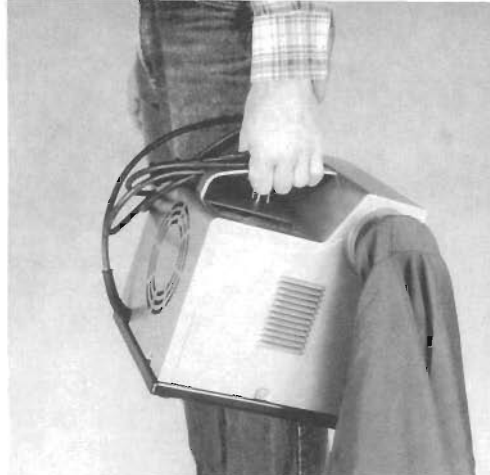
Mighty Midget: Weighing in at 20.4 pounds, the Makita 410 is the only collector you can pick up and carry around the shop. When running, the bag inflates to about 2 ft. in diameter and 30 in. long. The tiny box moves 310 CFM at 20 in. static pressure.
