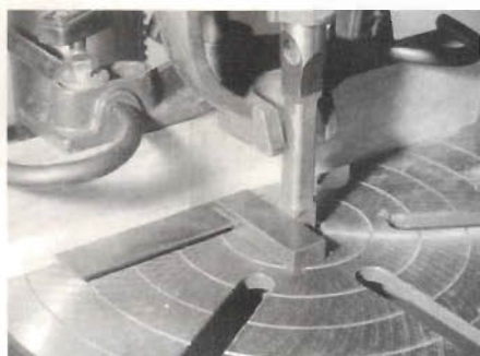
Photo 2: An engineer's square works well to square the chisel to the fence.
