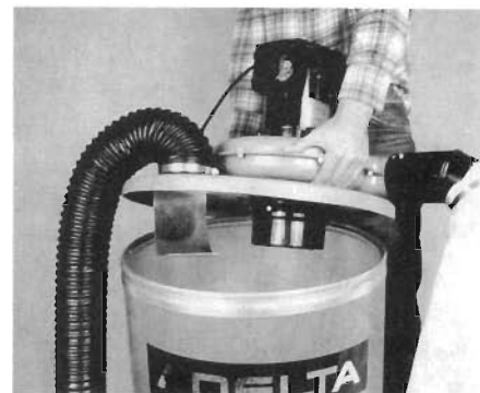
On two-stage collectors (Delta, Foley-Belsaw), you must remove the motor blower assembly to empty the waste barrel.
