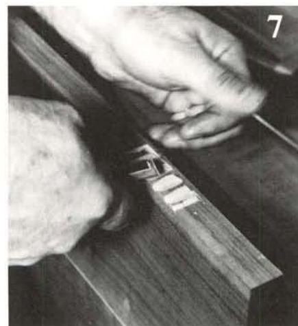
Photo 7: Use the corner of a small chisel to widen the kerfs as shown, cutting one side of the kerf and then the other. The chisel should be very sharp so you can pare away the waste without having to use excessive force. If you have to push too hard, you're likely to slip.
