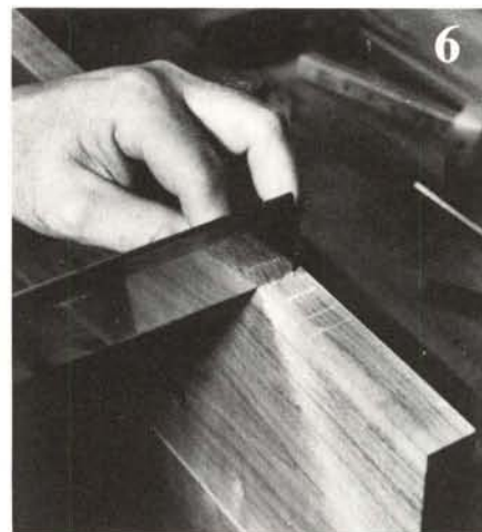
Photo 6: Use the dovetail saw to make a series of kerfs almost, but not quite, to your marked depth. First hold the handle of the saw down and make an angled cut from the depth line to the width line. Then slowly raise the handle as you work the saw, deepening the rear of the cut but staying within the mortise. Make the kerfs \frac{1}{4} in. to \frac{3}{8} in. apart.
