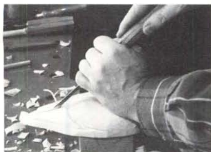
Photo 7: Pare away below the V-gouge cut.
