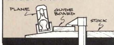
FIG. 5B A GUIDE BOARD CAN BE CLAMPED TO STOCK TO HELP ESTABLISH EDGE OF BEVEL.
