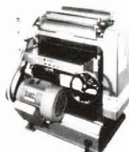
BRIDGEWOOD SHG-200A CABINET SHOP MODEL 20" x6" -3HP 220V
