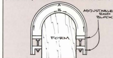
FIGURE 3 WITH ADJUSTABLE END BLOCKS STRESSES CAN BE RELIEVED. FIBERS AROUND OUTER ARC (A) STRETCH; INNER FIBERS COMPRESS.
