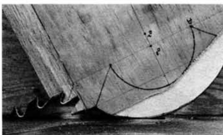
The panel is tilted in the opposite direction to remove waste along the other side of the arch.
