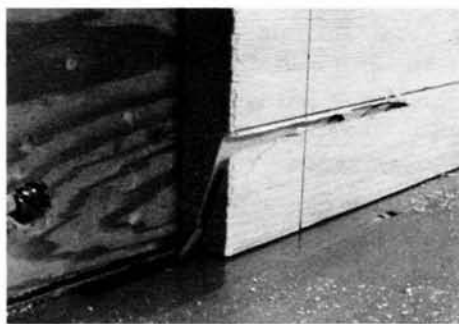
The initial cuts with the table saw blade at an angle, form the bevel along the sides and bottom of the panel.
