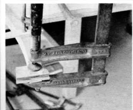
Photo B — Clamp applies pressure to face of joint when splines are glued in place. Note clamp pads are used to protect stock.
