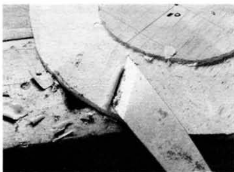
Paring the bevel around the arch.
