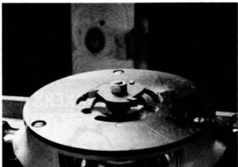
Photo shows router base with three wing carbide slot cutter. Pilot bearing is below cutter.
