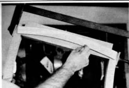
Photo F — Part I is dry fitted, then template is held in place and lines scribed.
