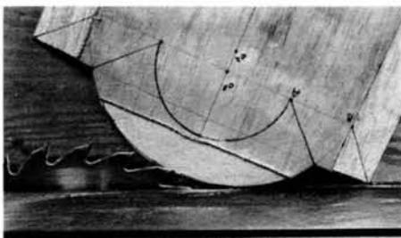
The arch is bandsawed to shape and the panel is tilted for the next cut which removes waste along one side of the arch.
