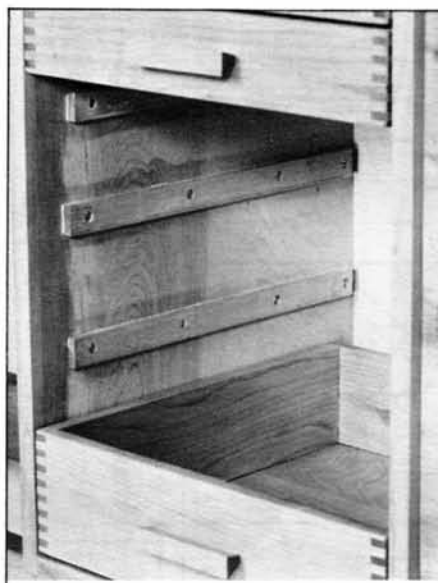
Drawer guides (Part X) are screwed to inside of carcase.
