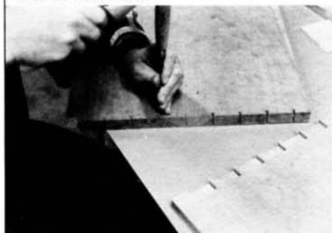
Waste material is removed with a mallet and small sharp chisel.
