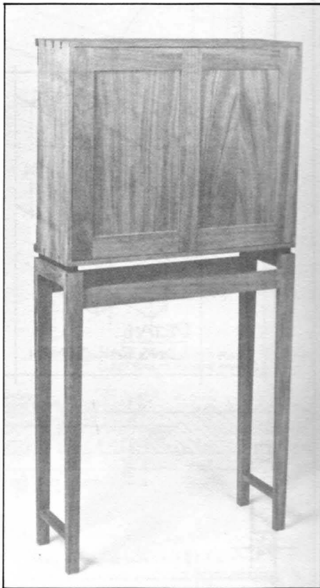
Rear view displays framed panels of book-matched rosewood. Note that, unlike doors, stiles run from top to bottom with rails butting against them.
