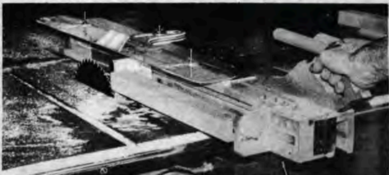
Photo shows jig with guard in place, using a 10" carbide tip sawblade, preparing to cut 2" x 2" x 24" stock. Centers are 1/4" Tee nuts driven into each end.
