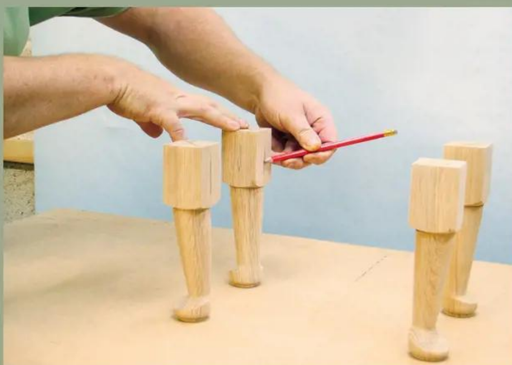
3 Stand the legs in their final positions and mark the faces that need mortising
