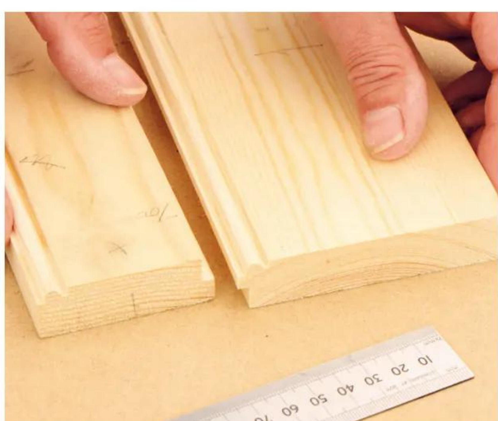
7 Experiment with bearing-guided beading and rebate bits on offcuts in order to achieve the correct depth
