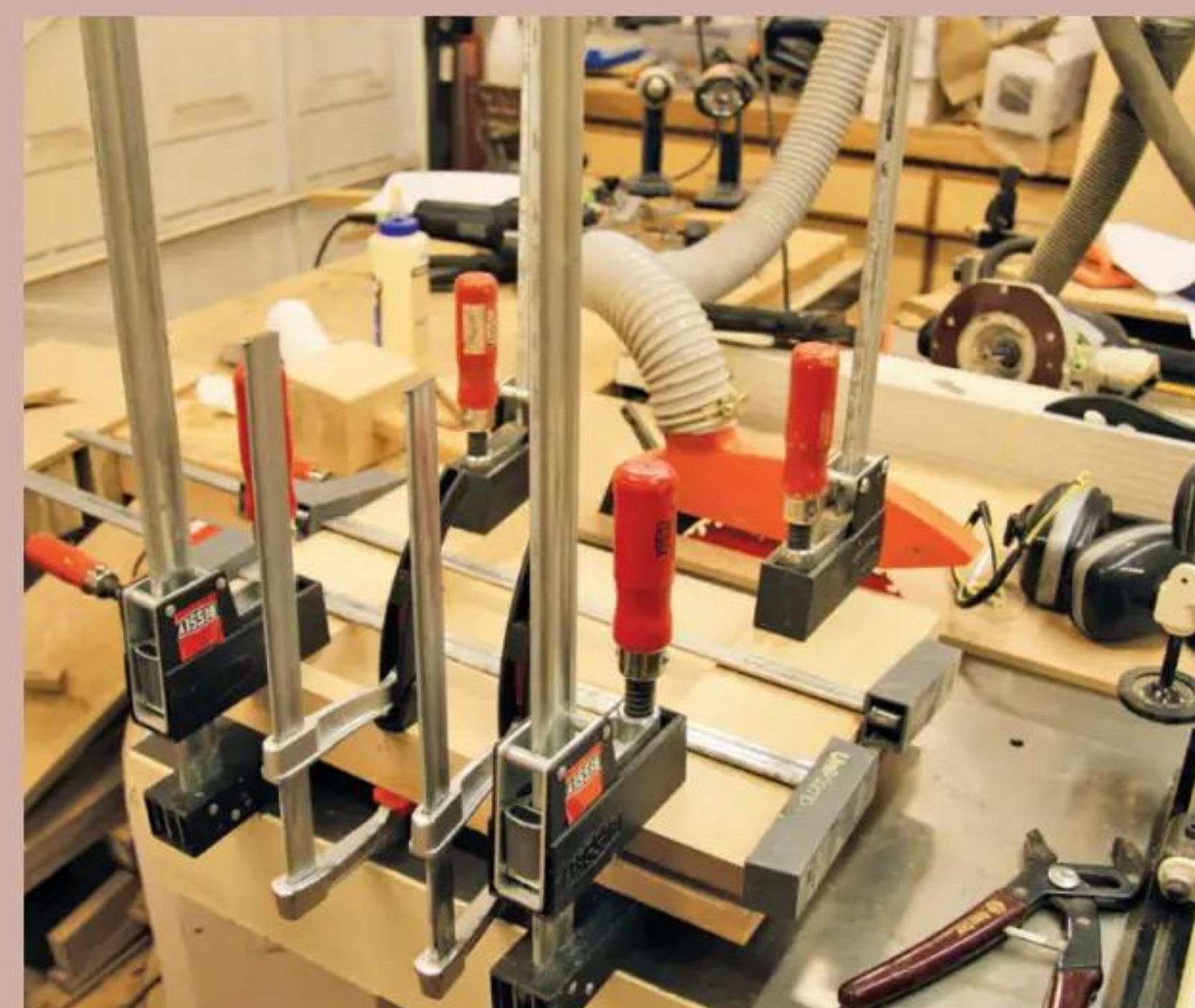
6 The bottom assembly was glued together in advance of the remaining piece
