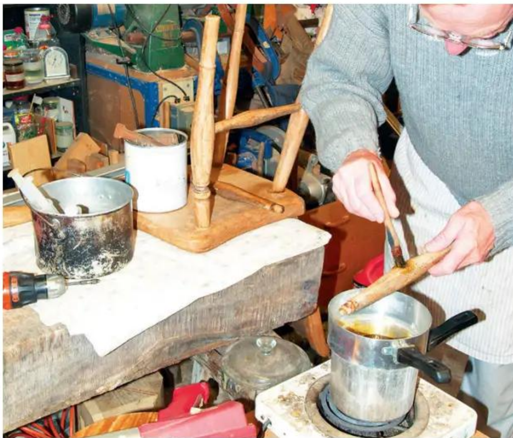
2 Start by gluing up the stretcher; you only have 60 seconds to finish the assembly, so ensure to work quickly
