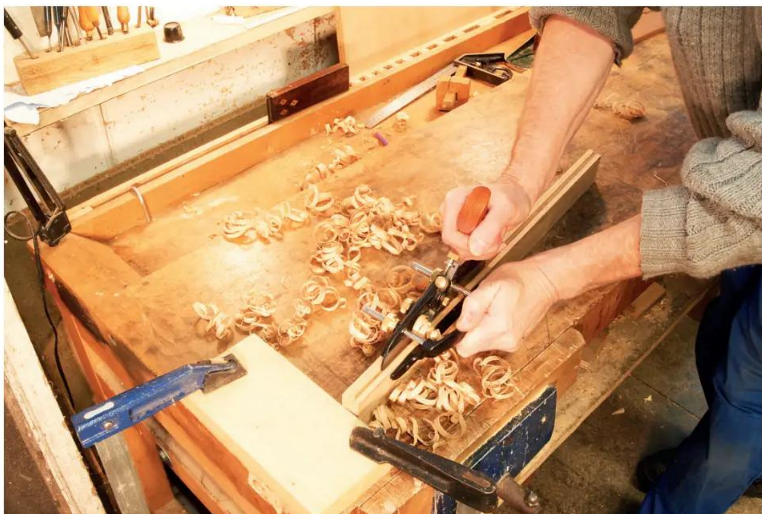
12 Ploughing a groove with a speciality plane
