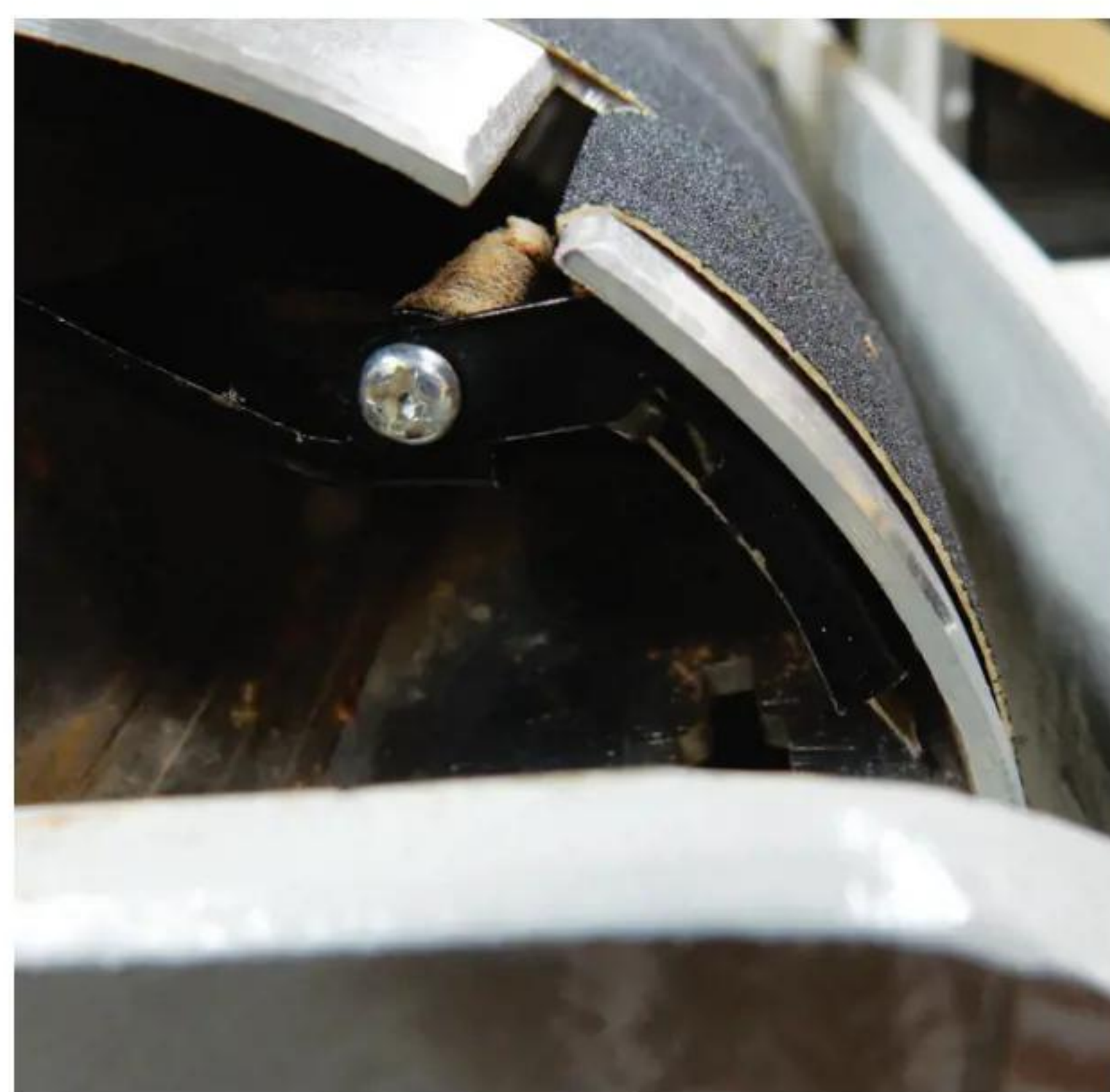
4 The belt's tapered end is inserted into a sprung clip located on the drum's left-hand side
