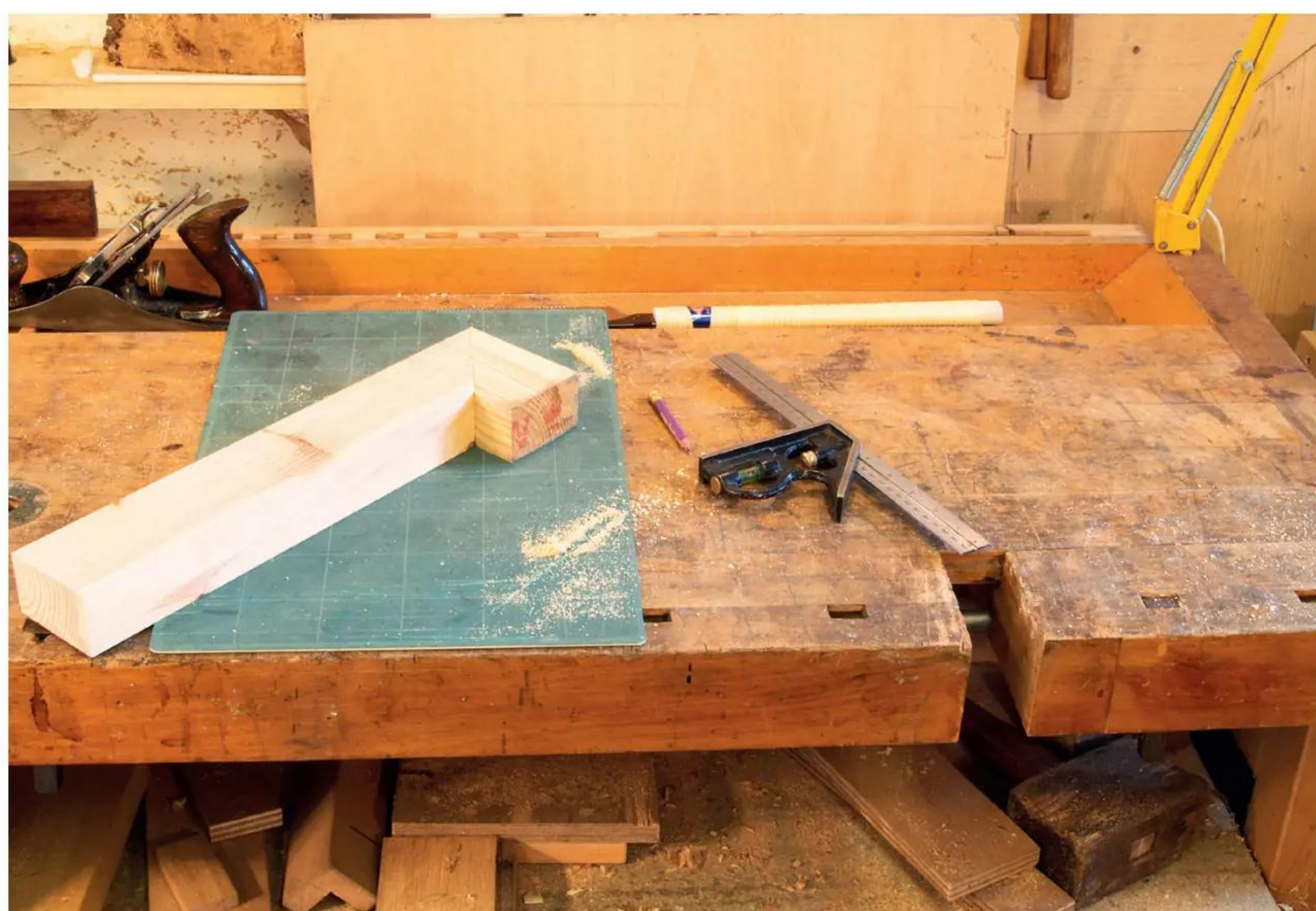
3 A couple of passes with a plane and the butt mitres are finished, but dowels or biscuits are required
