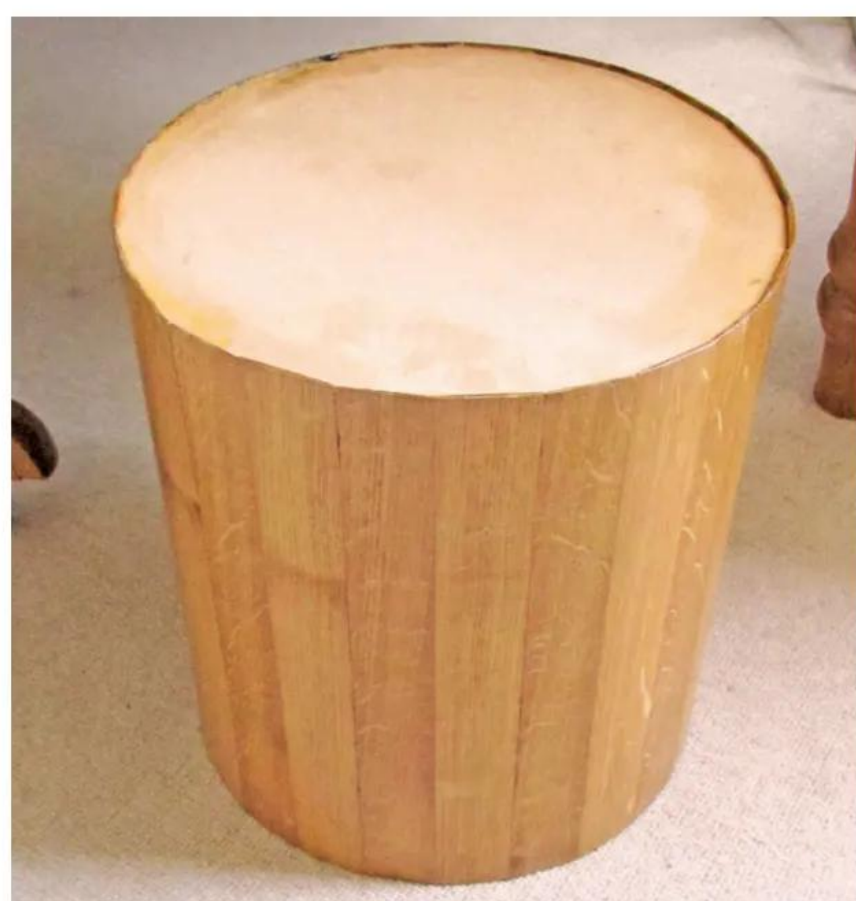
2 The base is hardboard let into a 3mm rebate. Use the glued-up cylinder itself as a template in case it's not exactly round
