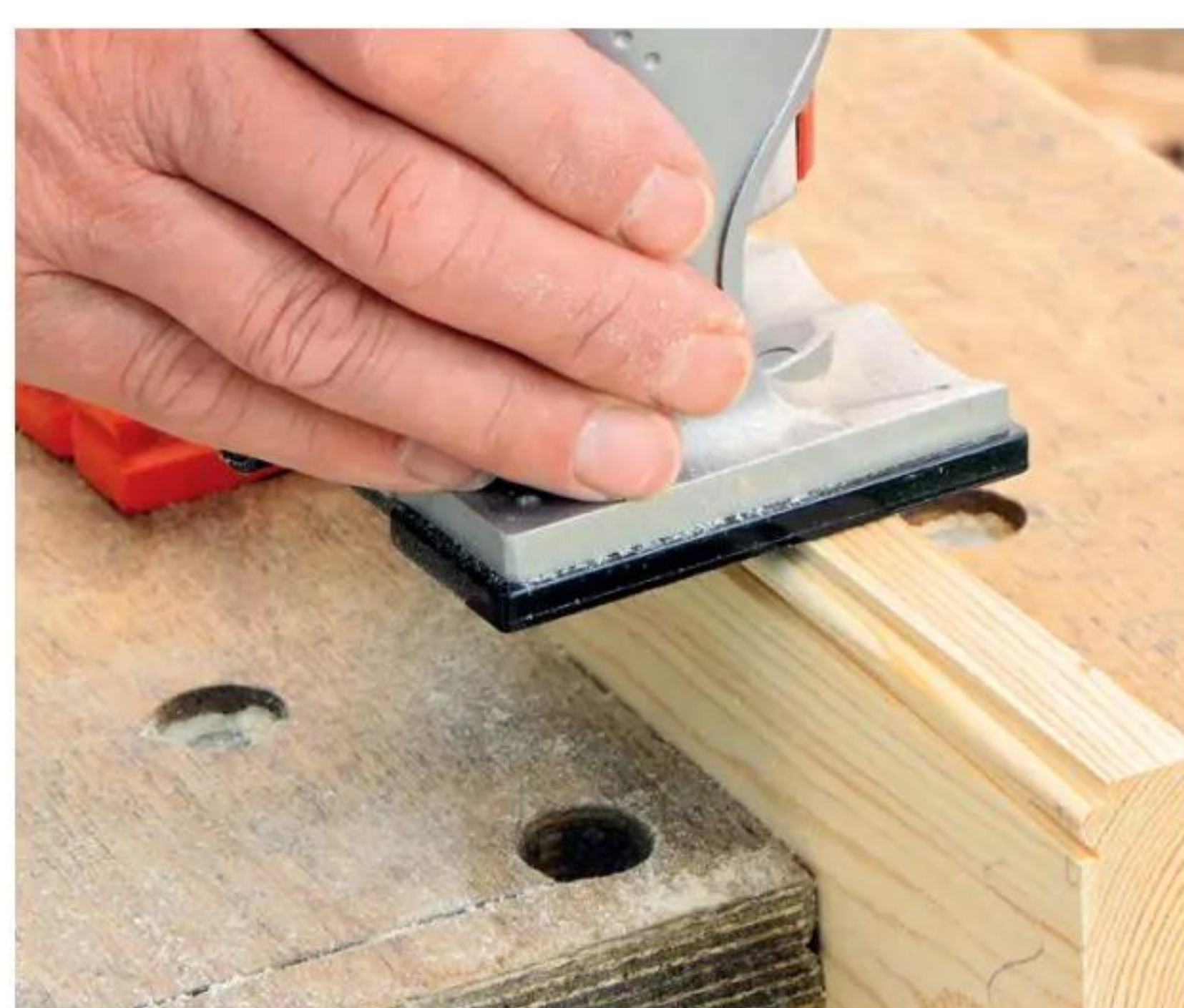
8 Rout the beading profile along the board edges; cramp timber to support the router if necessary
