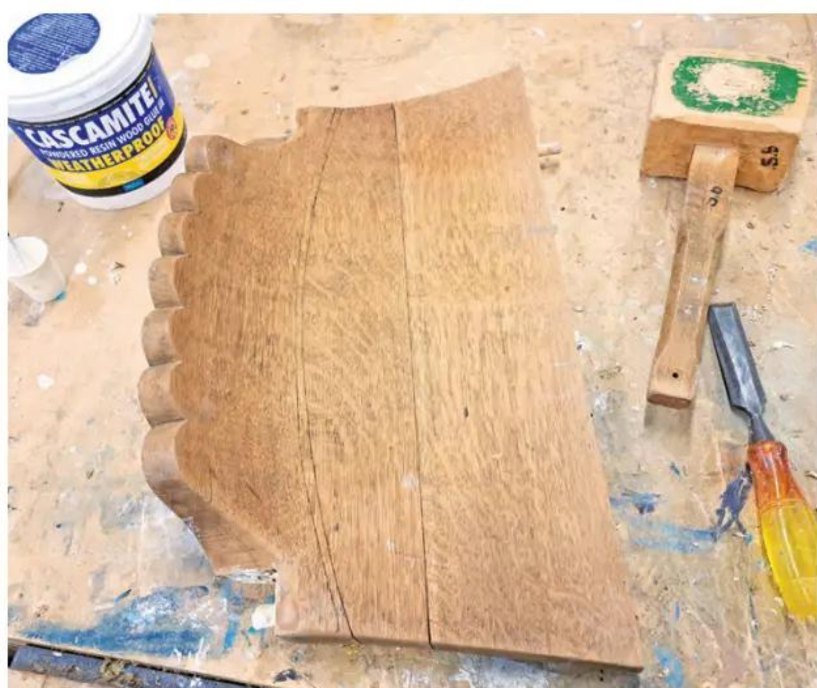
4 The seat base was re-glued after carefully cleaning off all traces of animal glue
