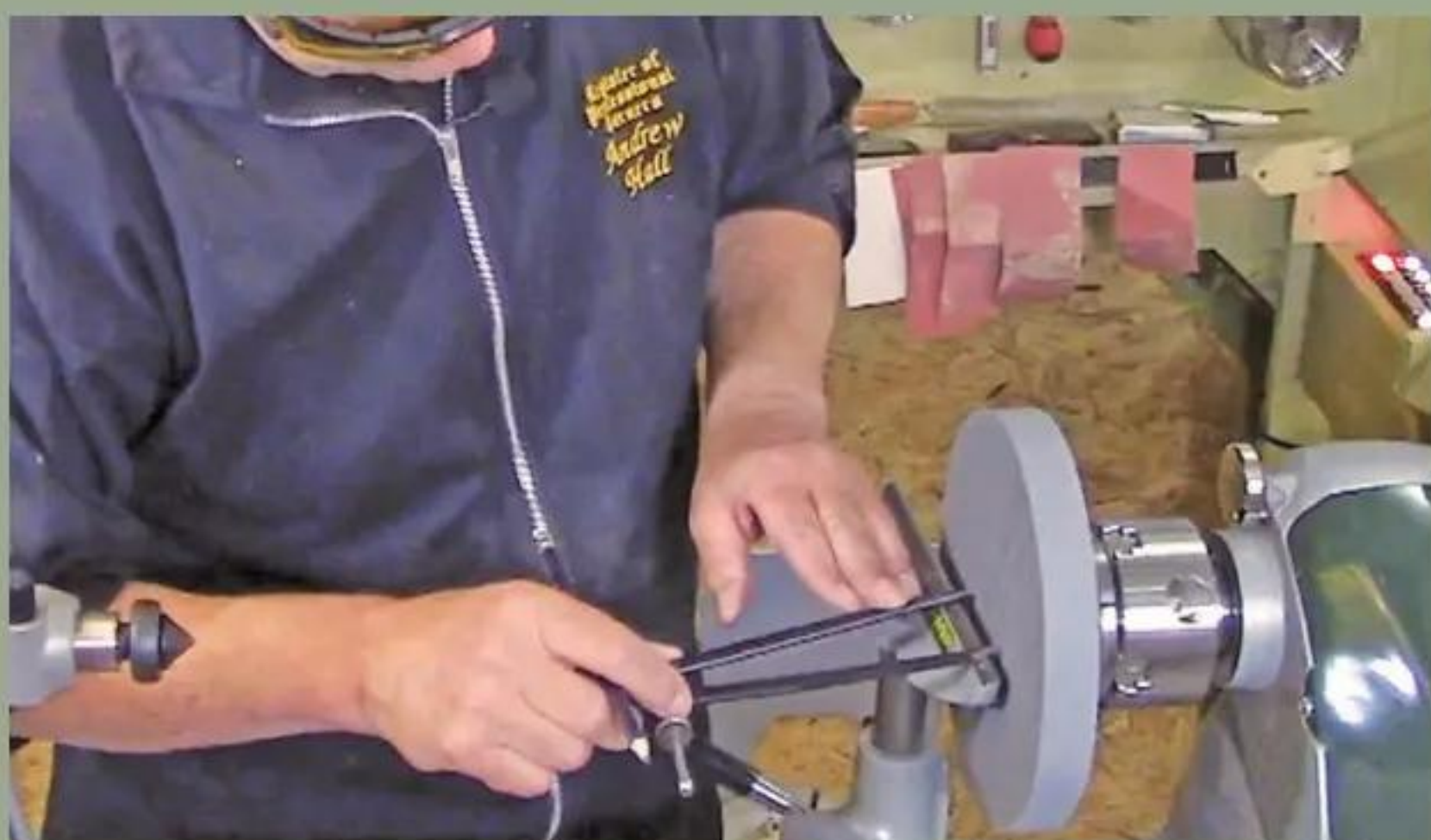
38 Using the dividers, I sized the optimum circle size and marked the tenon diameter with a pencil
