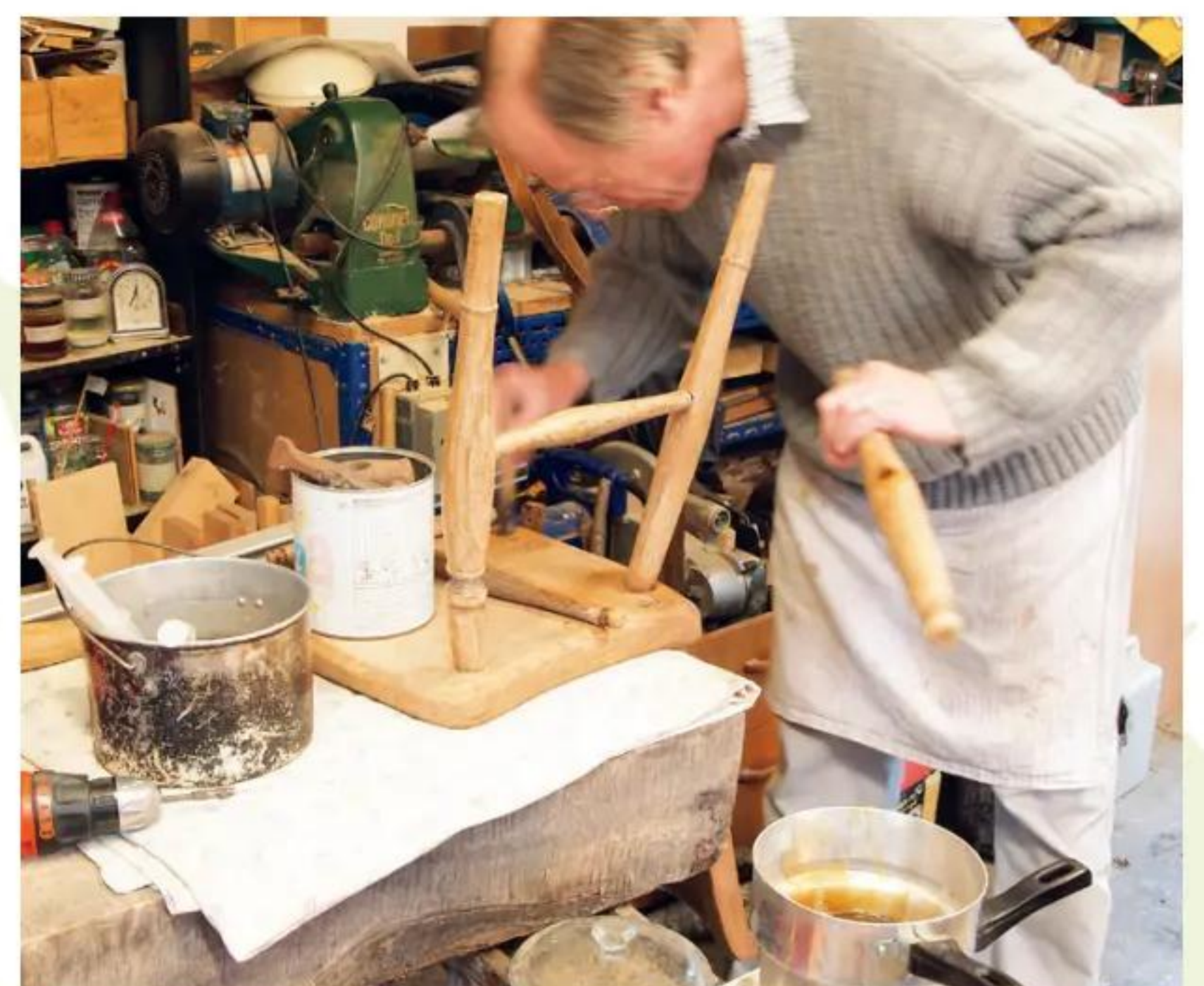
6 ... and leg mortises, but remember the stretcher is drying, so work fast
