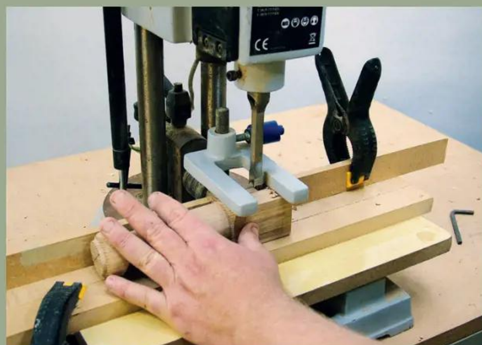
4 Set out the top and bottom of each mortise and cut them all on a bench mortiser
