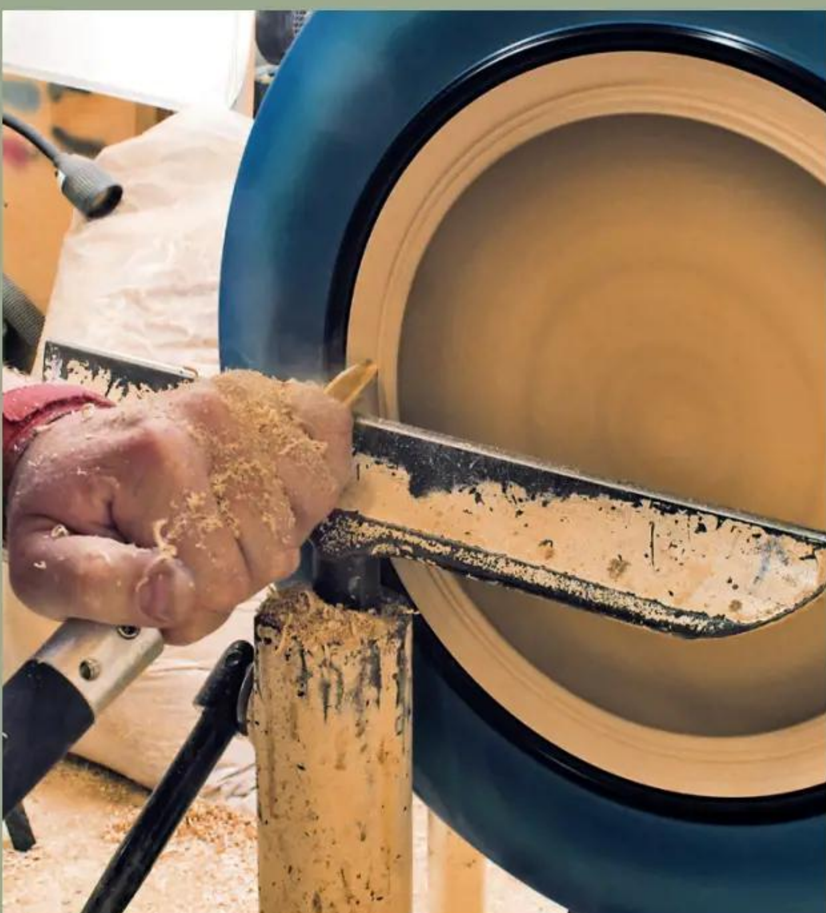
19 Turning the inside is just like working on a normal bowl; start from the outer edge and finish each stage as you go, using the 10mm bowl gouge in push-cutting mode
