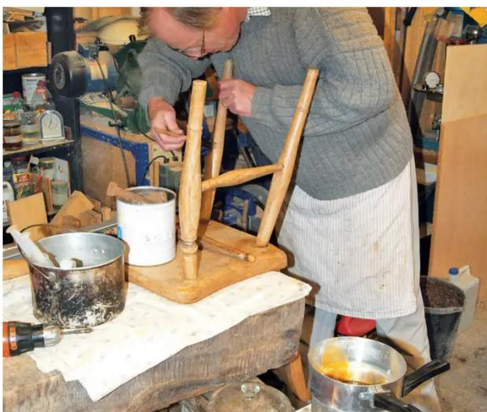
4 Set the stretcher assembly aside in the correct alignment and apply glue to the rail mortises...
