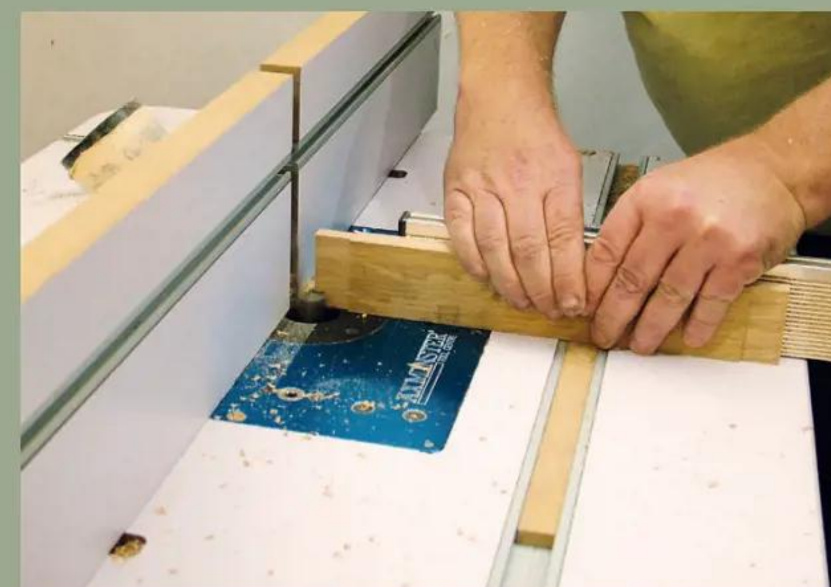
5 Cut the corresponding tenons on the router table, then add their haunches
