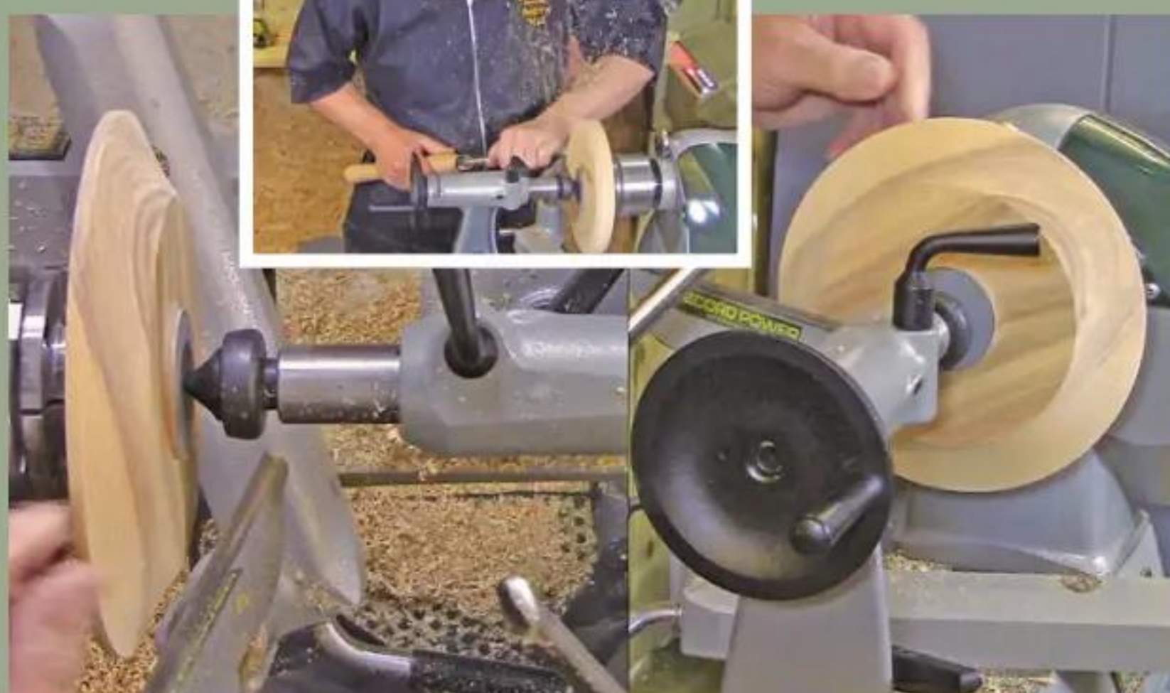
42 Using the swept-back gouge and lowering the back hand, cut a chamfer one-third of the platter width, leaving an edge of approximately 10mm
