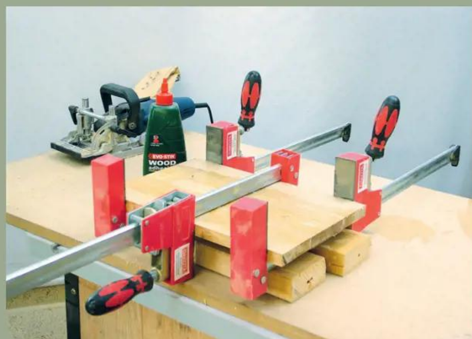
2 Glue and cramp up the three boards as shown and set them aside to dry
