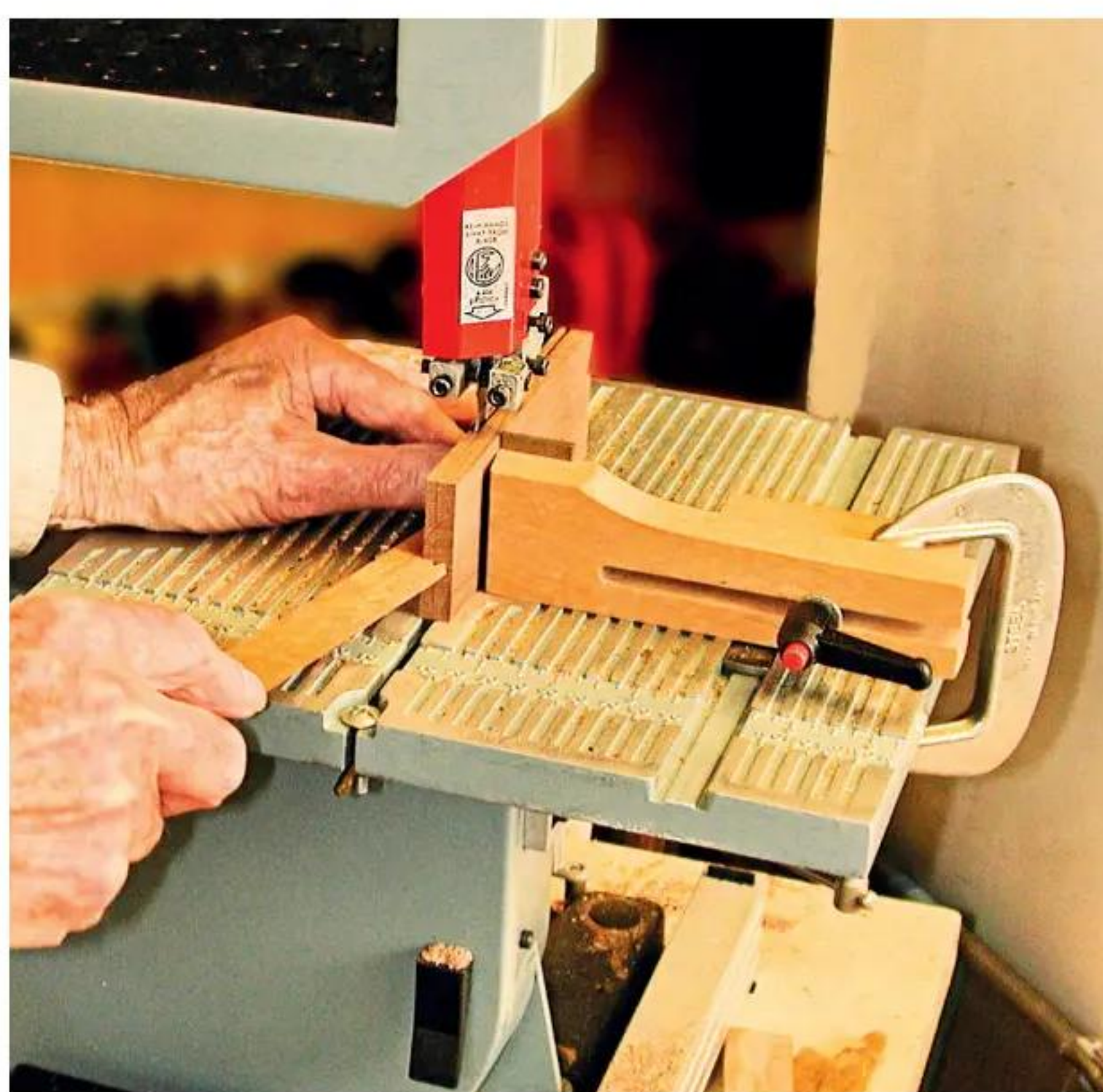
4 I safely re-sawed the sides using my workshop-made point fence
