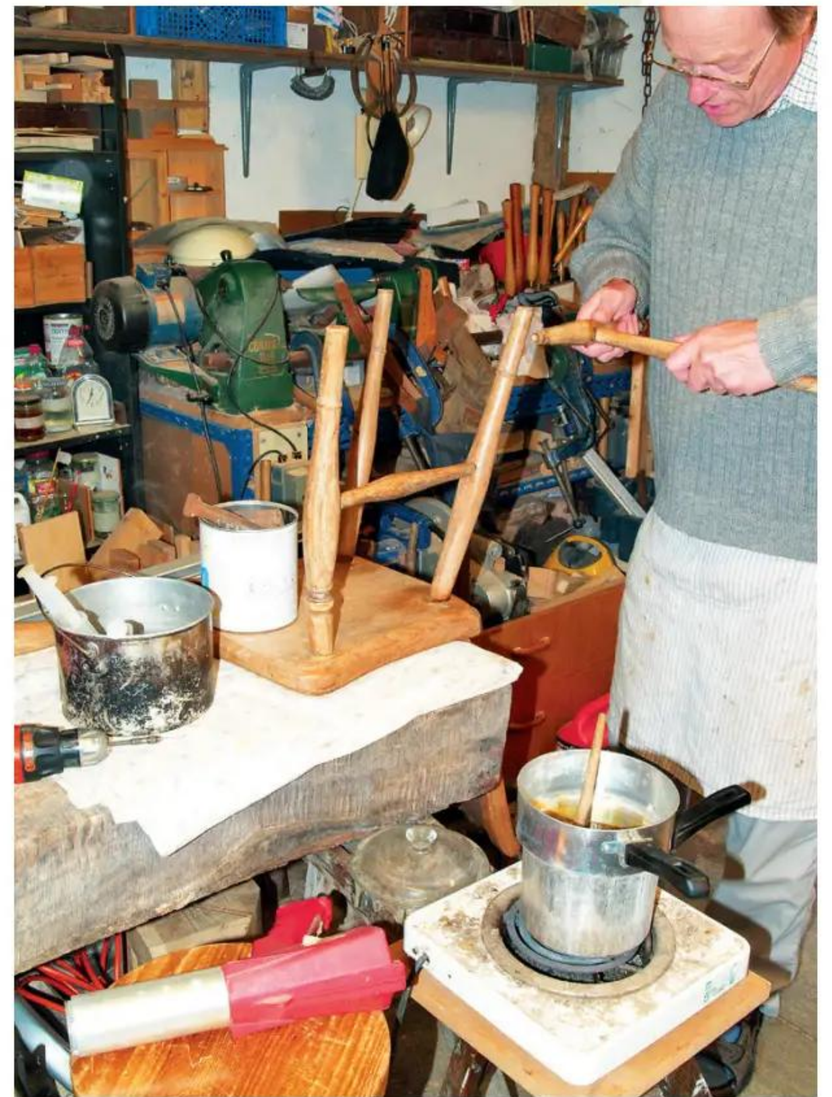
3 Side rail to stretcher: if re-gluing an old chair, ensure the stretcher is correctly aligned, worn surface upwards
