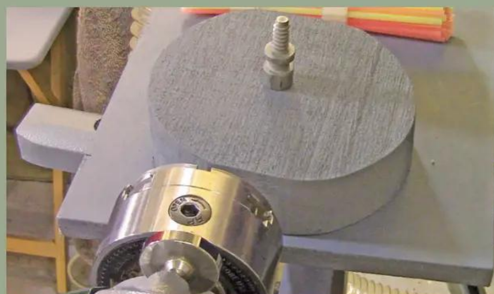
3 A worm screw or screw chuck – the most common method of holding a side-grain blank – which fits into the chuck jaws
