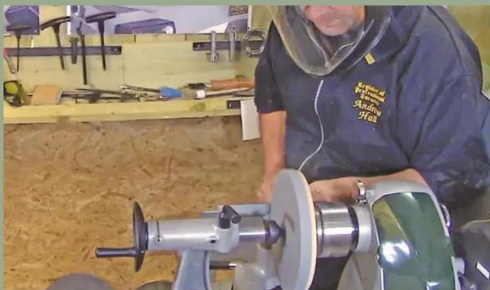
39 Work from left to right halfway across the blank, then right to left in order to prevent breakage on each edge. True up the blank to as large a diameter as possible, in this case using the swept-back bowl gouge
