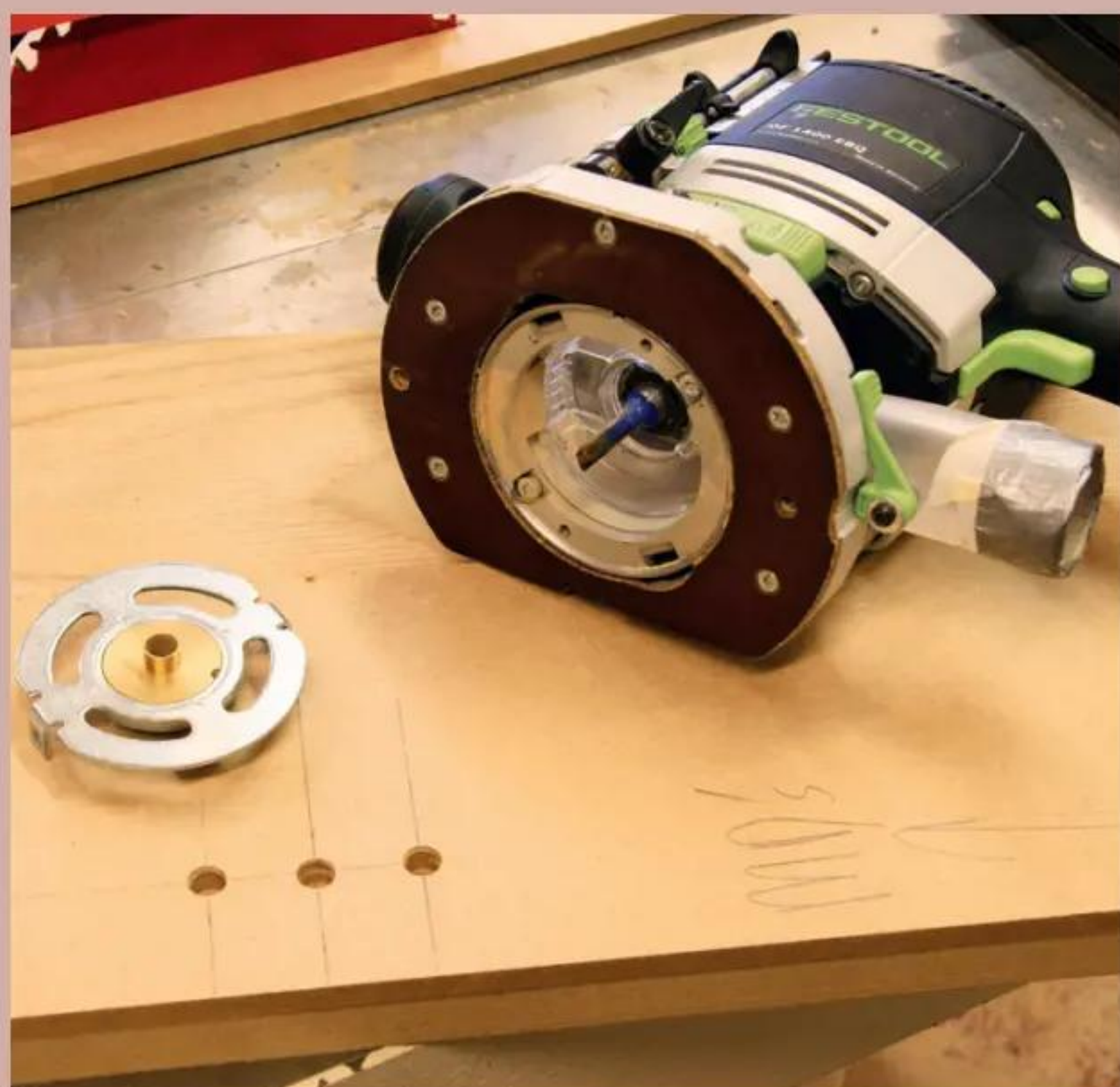
4 A guide bush is used with a plunge router for accurately machining the holes
