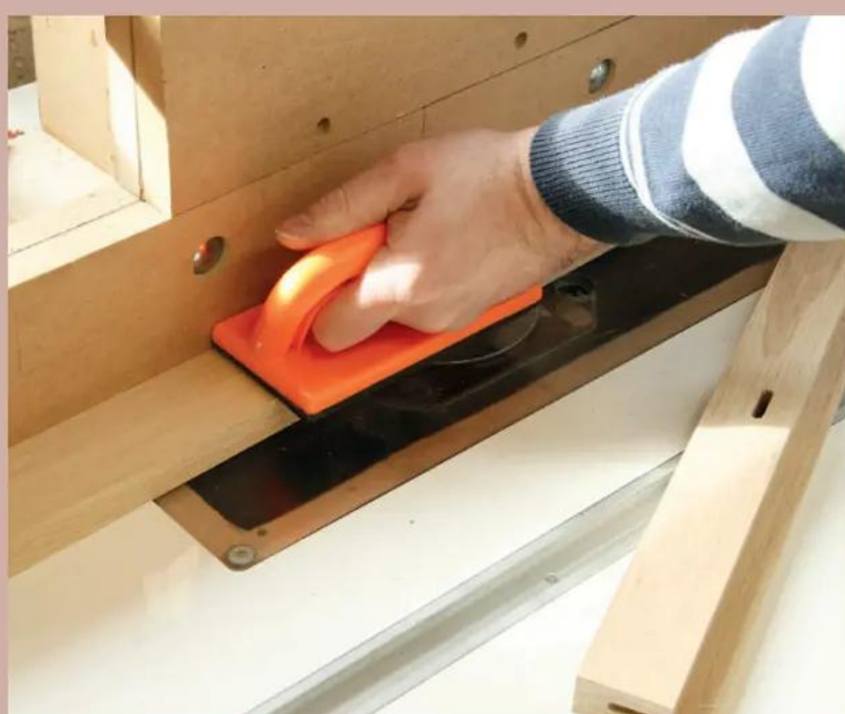
13 Rear frame sections were rebated to accommodate the back panel
