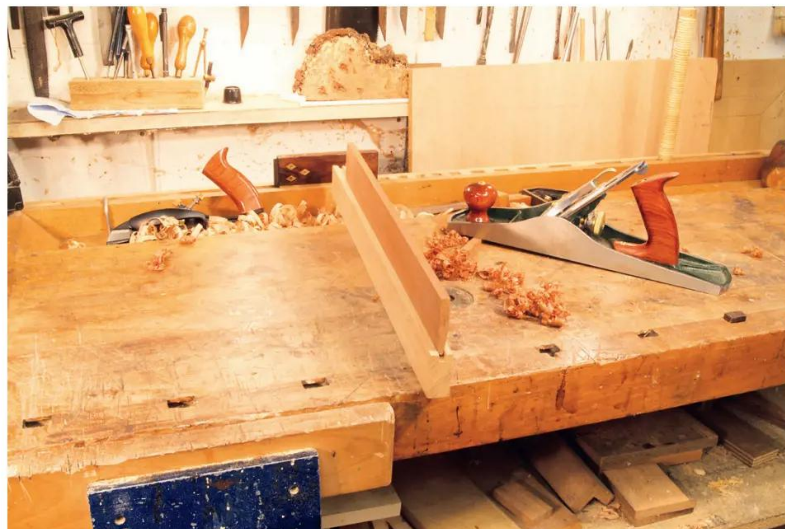
13 A fielded panel inserted into the groove; note that it doesn't extend to the groove's bottom
