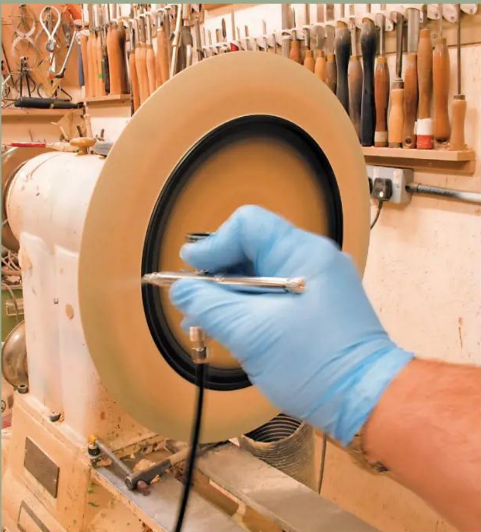
16 After filling up the little pot with blue stain, I start spraying the surface. Here, the lathe is set to a slow speed and the paint is started off the rim, then traversed across the surface
