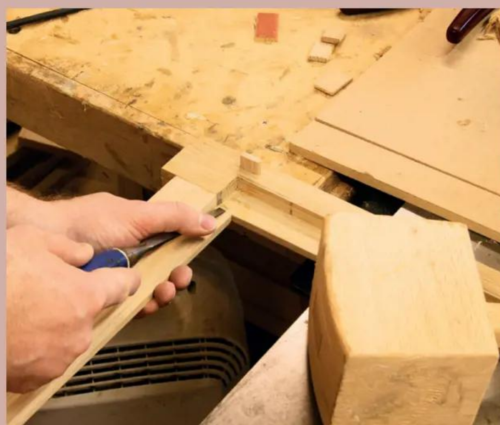
16 I cleaned up the rear panel rebates with the aid of a sharp chisel
