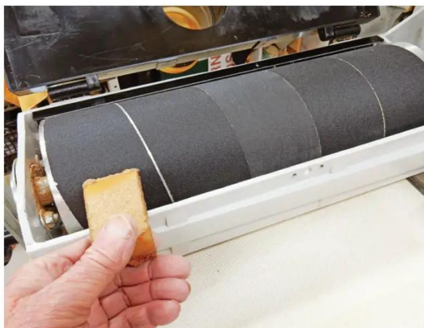
7 Following use, in order to keep the belt clean, a rubber block is used with the lid open, the drum rotating and dust extraction running
