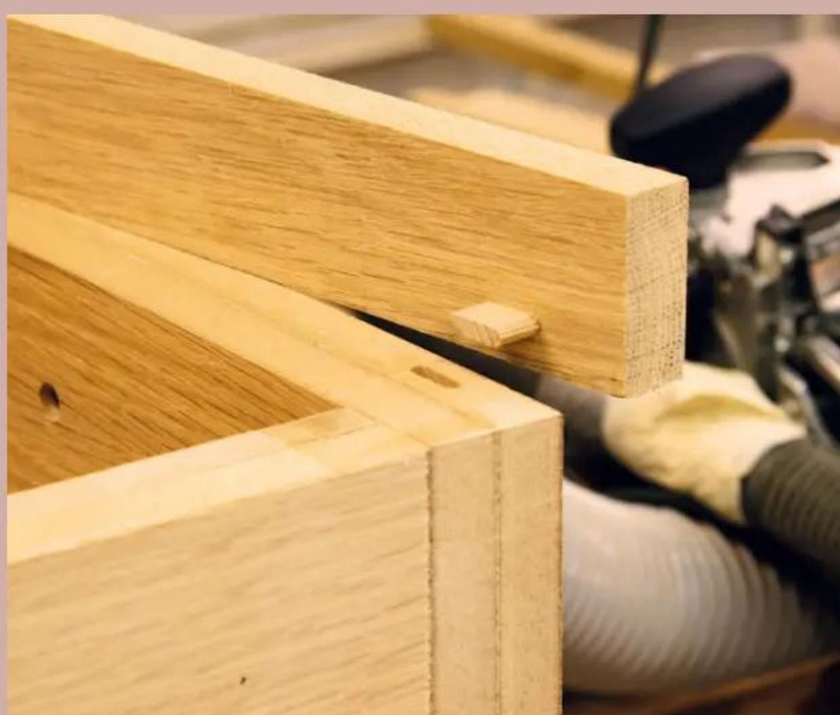
11 The frame has Dominos cut at an 11mm depth for a 1mm overhang
