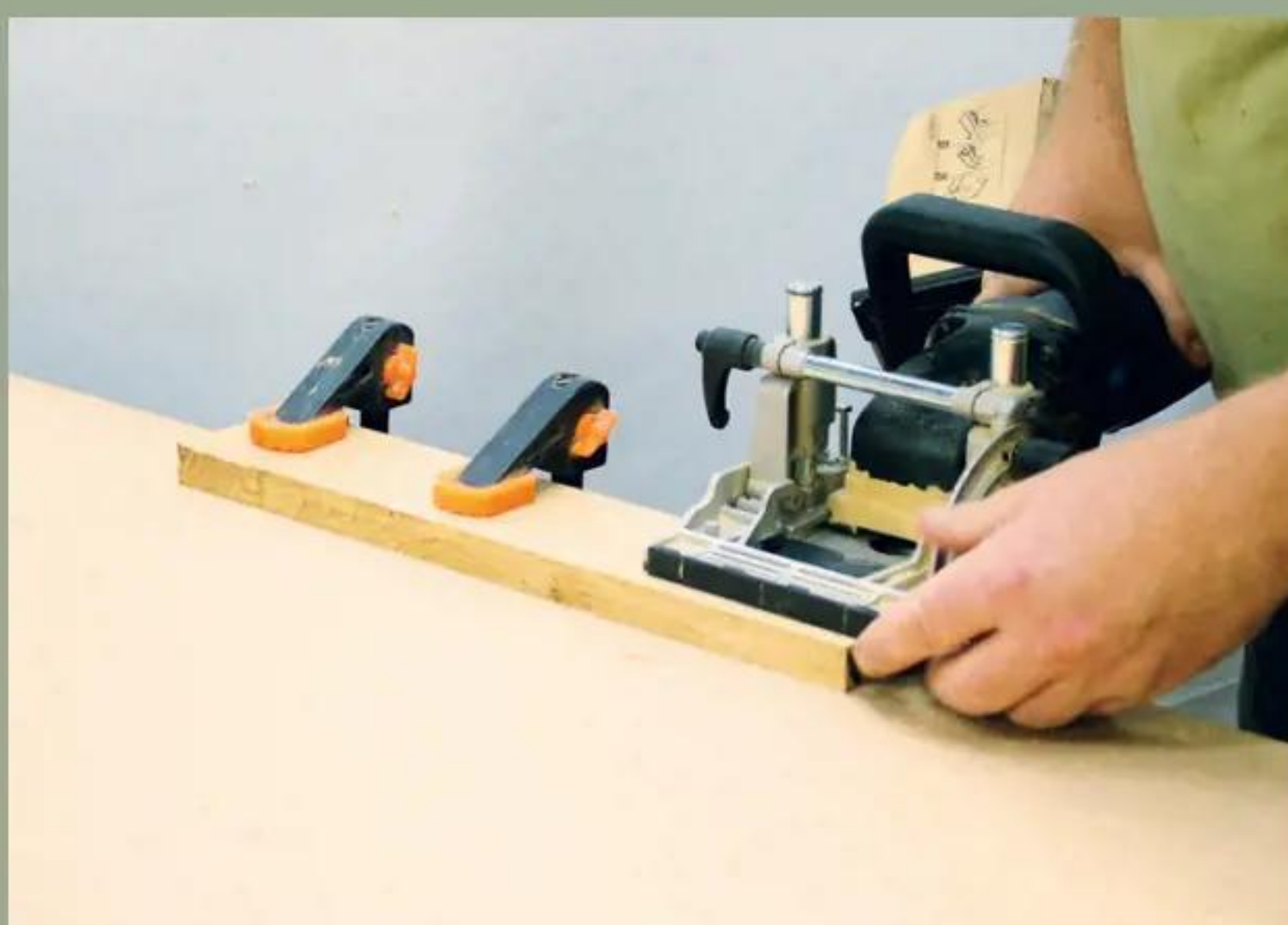
1 I decided to cut biscuit slots in the top board edges to reinforce the butt joints
