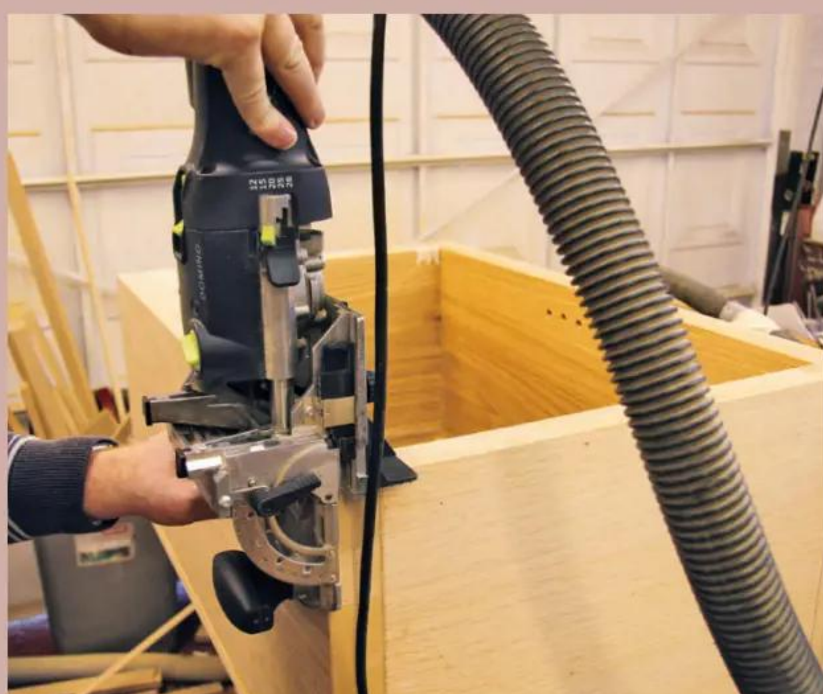
10 The carcass has Dominos cut 10mm in from the edge
