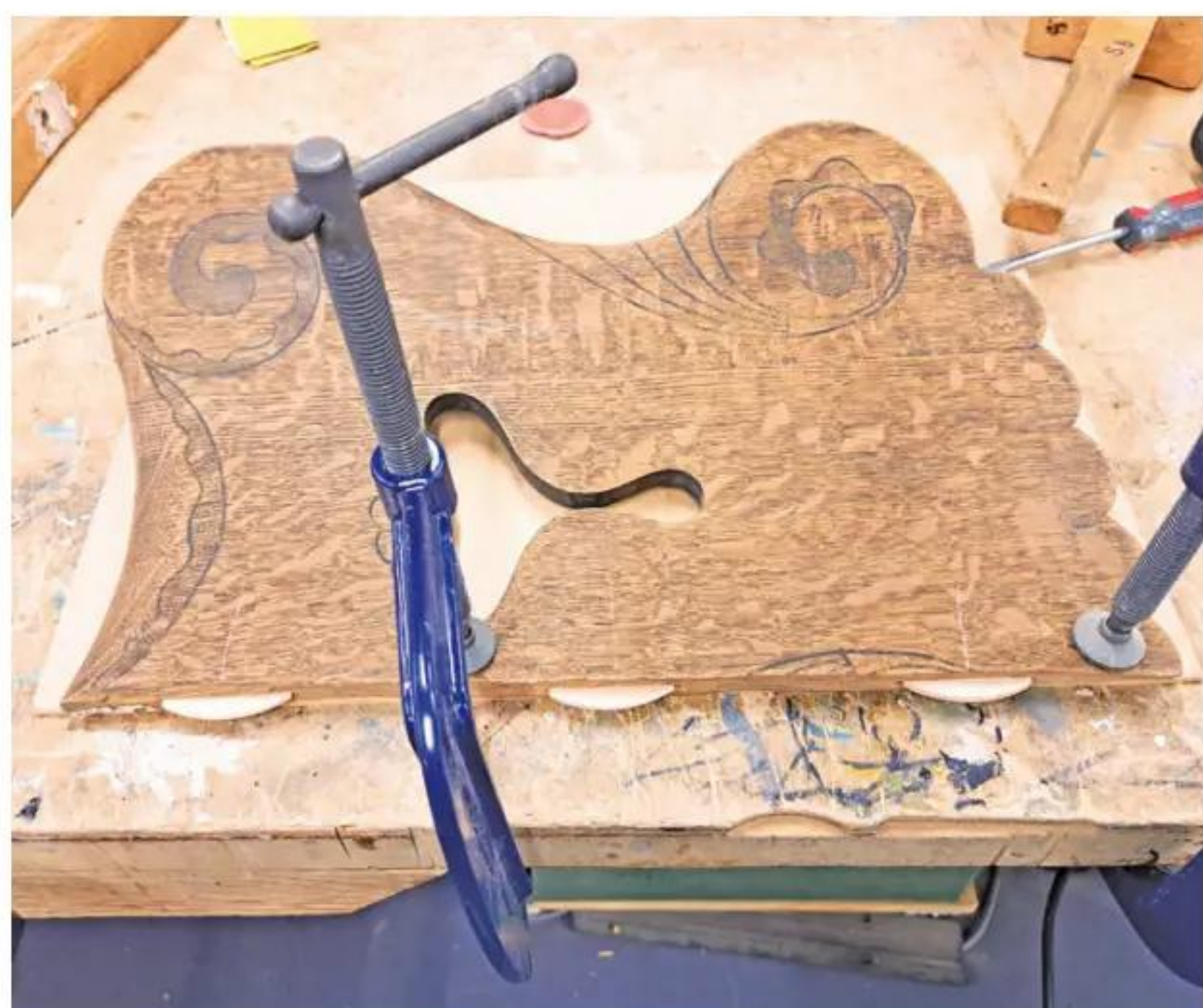
2 Biscuits are used to reinforce the joint and aid board alignment
