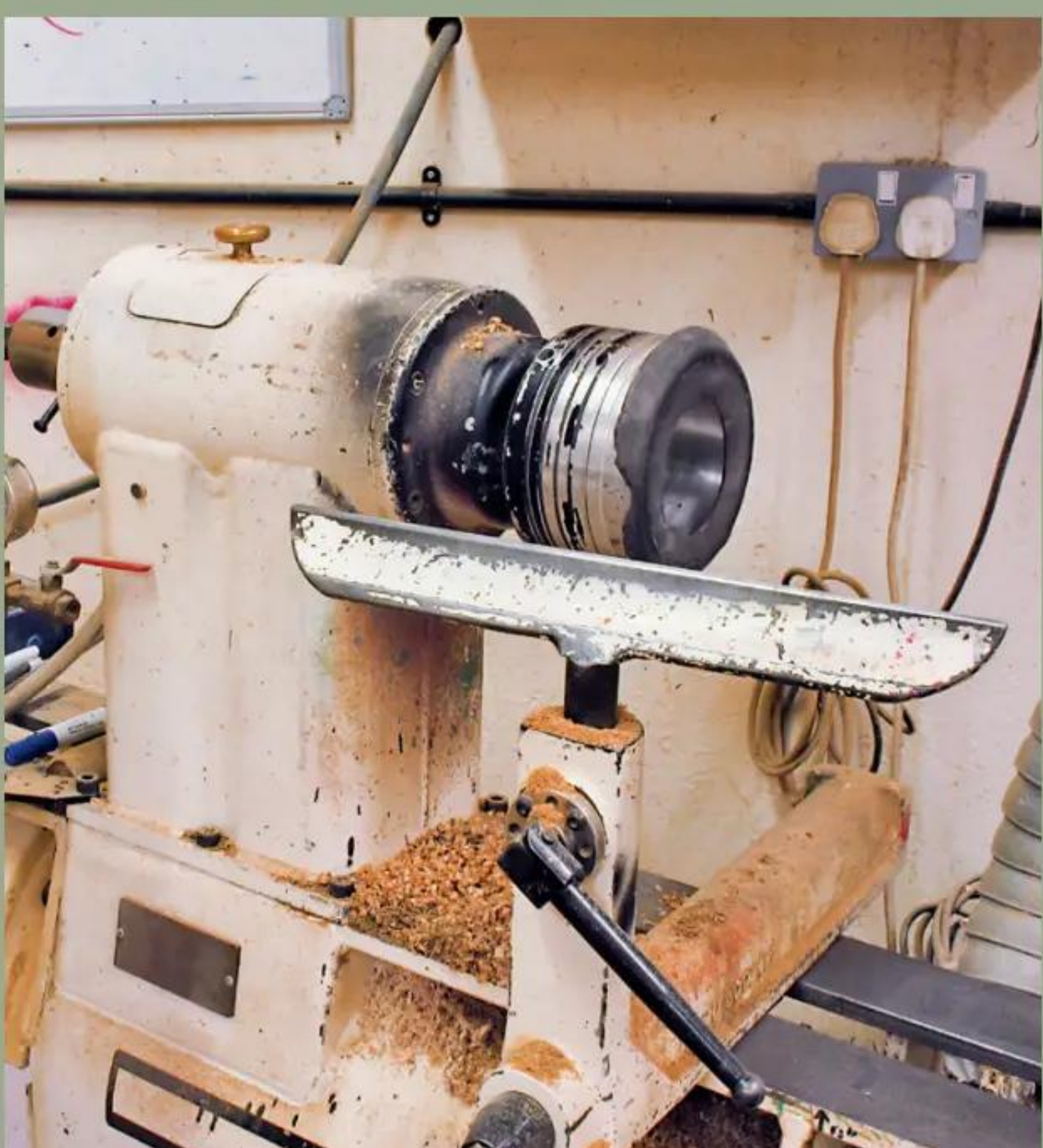
24 My vacuum chucking system allows me to remount the platter. This way, I can turn the spigot in order to remove the chucking marks
