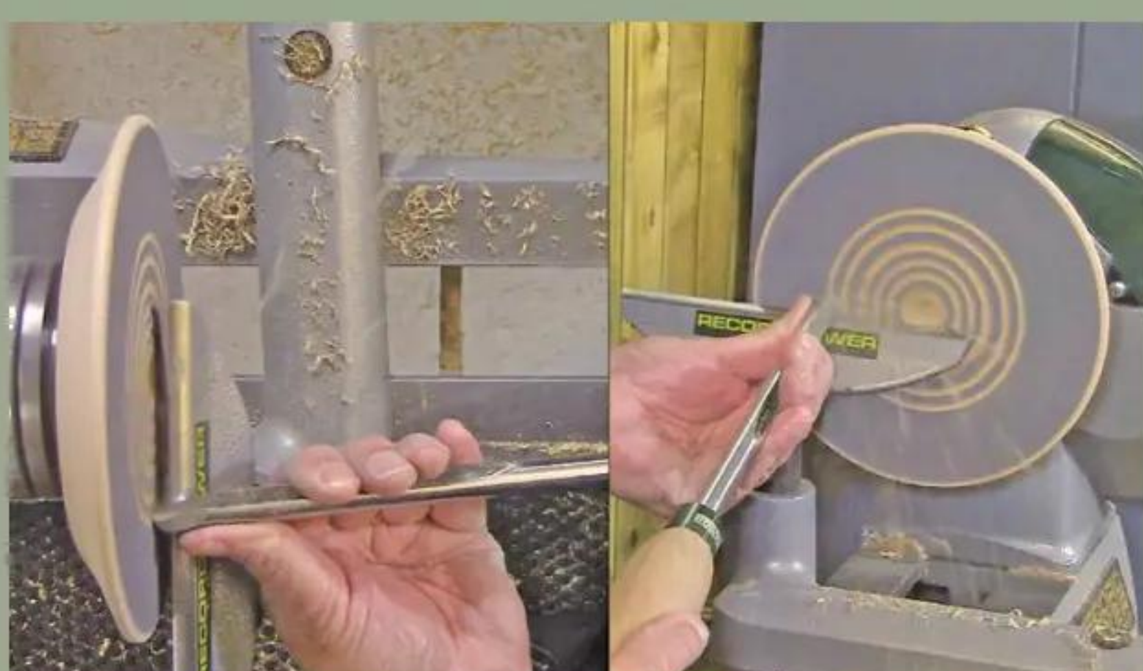
44 Reverse the platter blank and cut a series of 'V' cuts; this allows bevel contact as well as preventing skate back
