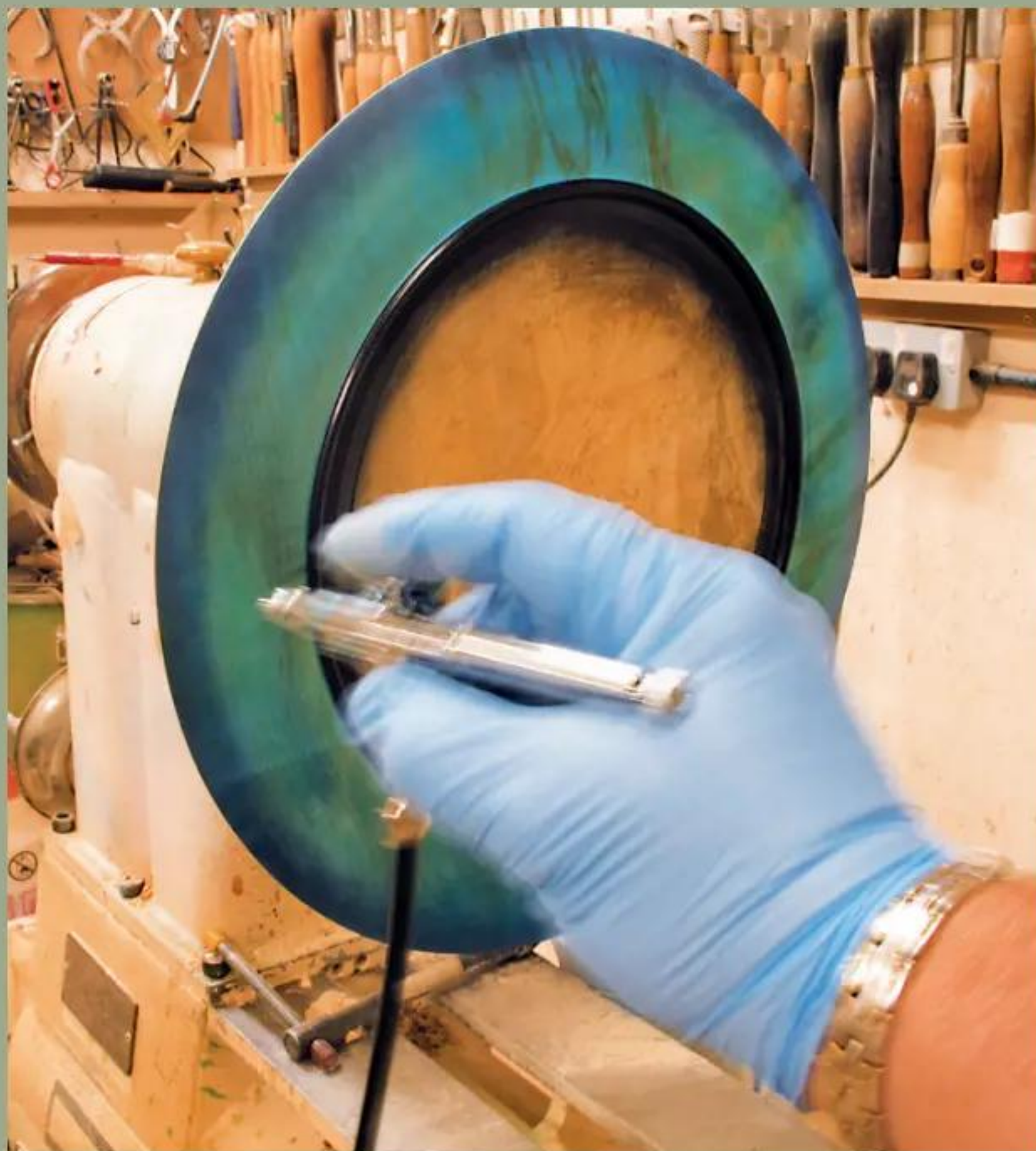
17 When the blue is dry, you have the option to shade in the edges with another colour. Here, I'm using royal blue to define the inner and outer edges; the satin won't show up on the black bead
