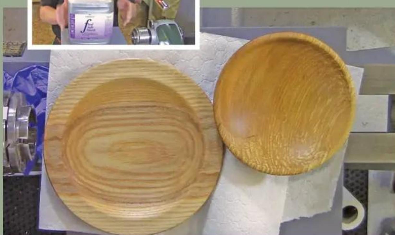
51 I used Chestnut Products' food-safe finish as the bowl and platter are utilitarian. I applied two coats of food-safe oil, leaving 24 hours between each coat, before buffing up with a safety cloth ✂
