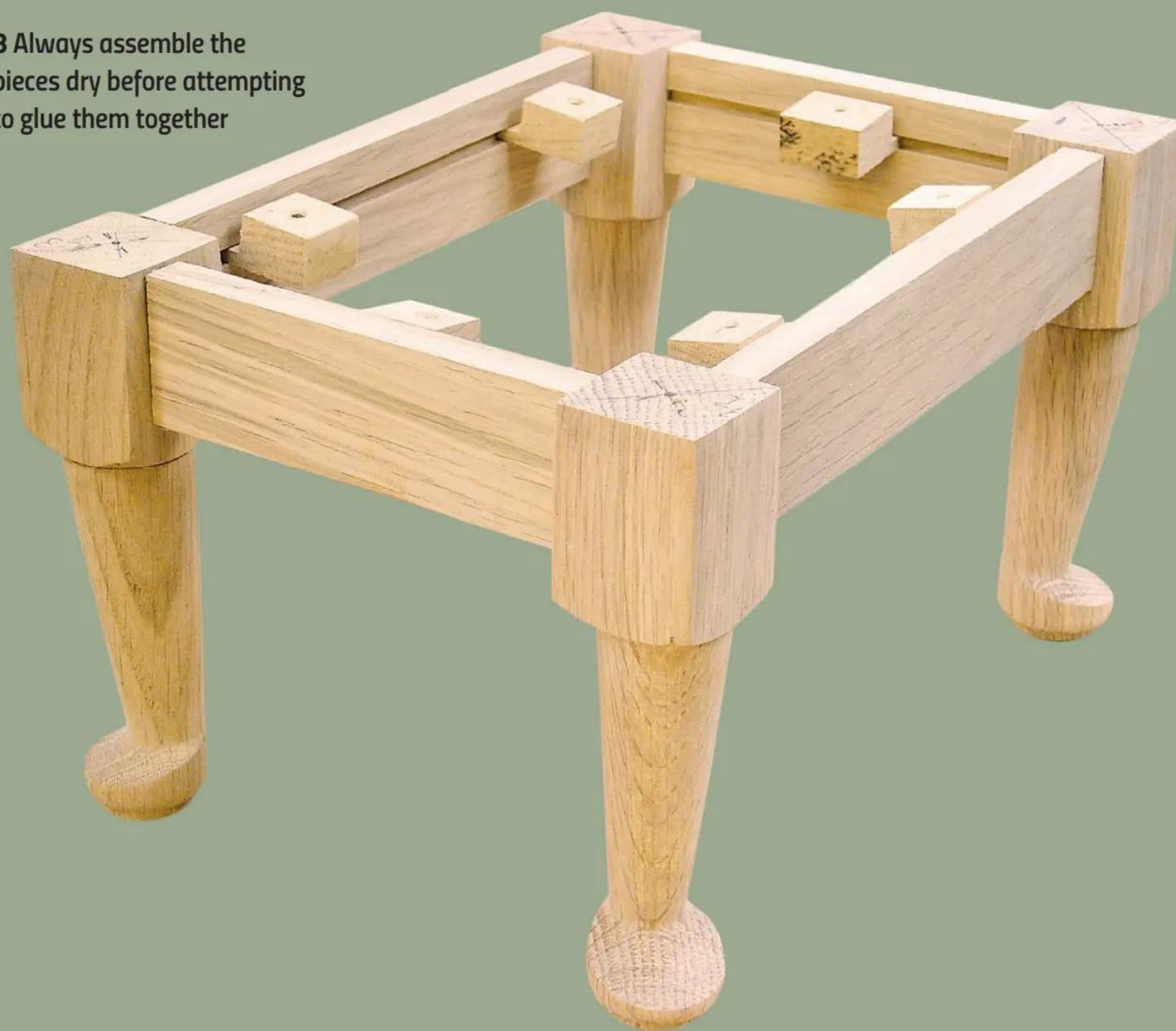
Fig.1 Cabriole stool assembly – showing how the screw blocks are used
