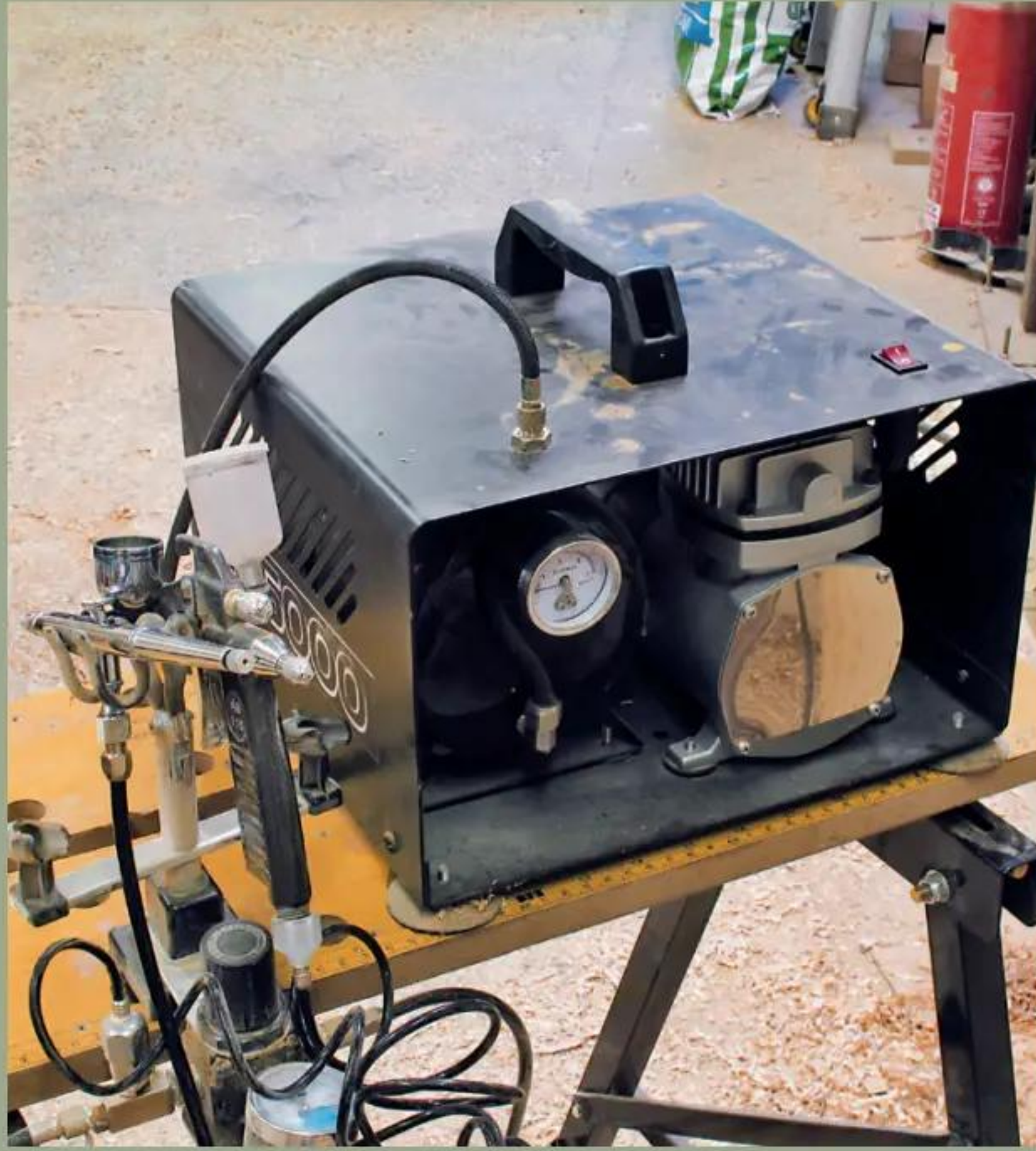
14 My airbrush setup came as a complete kit from Graphics Direct. Having a dedicated compressor means that there's no need to fit regulators into the workshop supply
