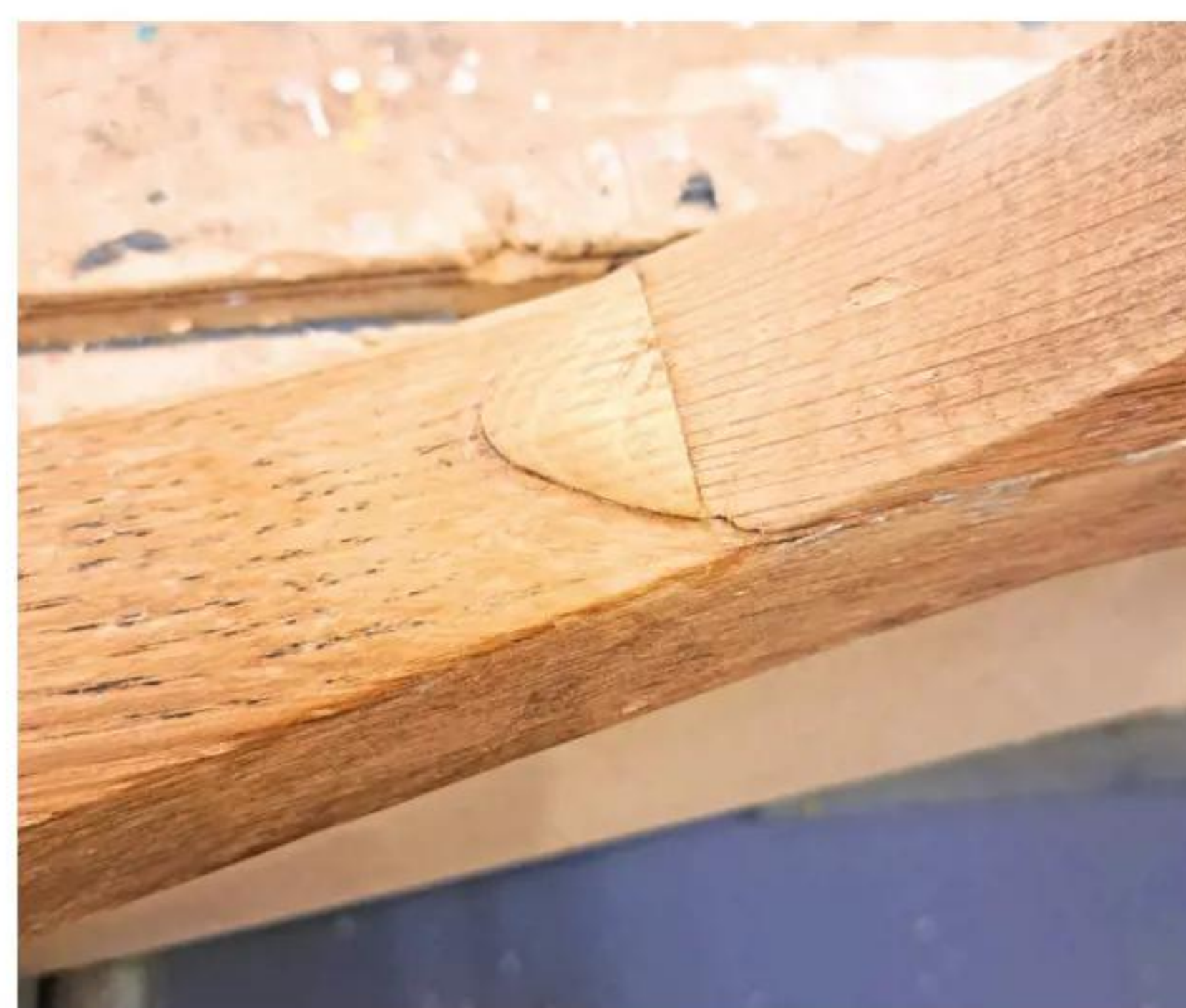
7 The arm was repaired by gluing in a fresh piece after roughly carving it to shape
