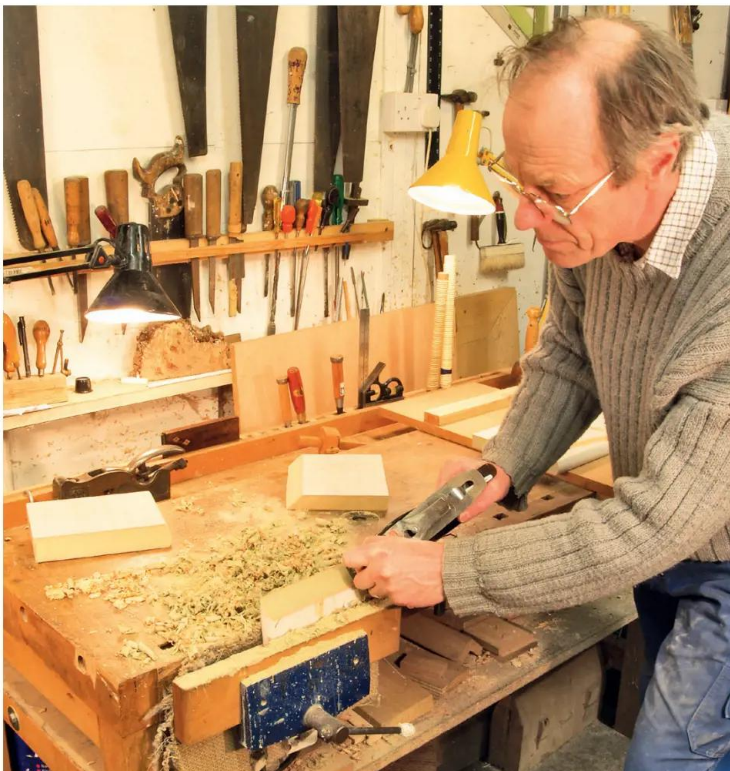
7 Planing in the sawn mitres for a home-made mitre box. This is MDF, which I don't like because of the dust, but is perfect for jigs because it doesn't warp. However, ensure to take dust precautions when using it
