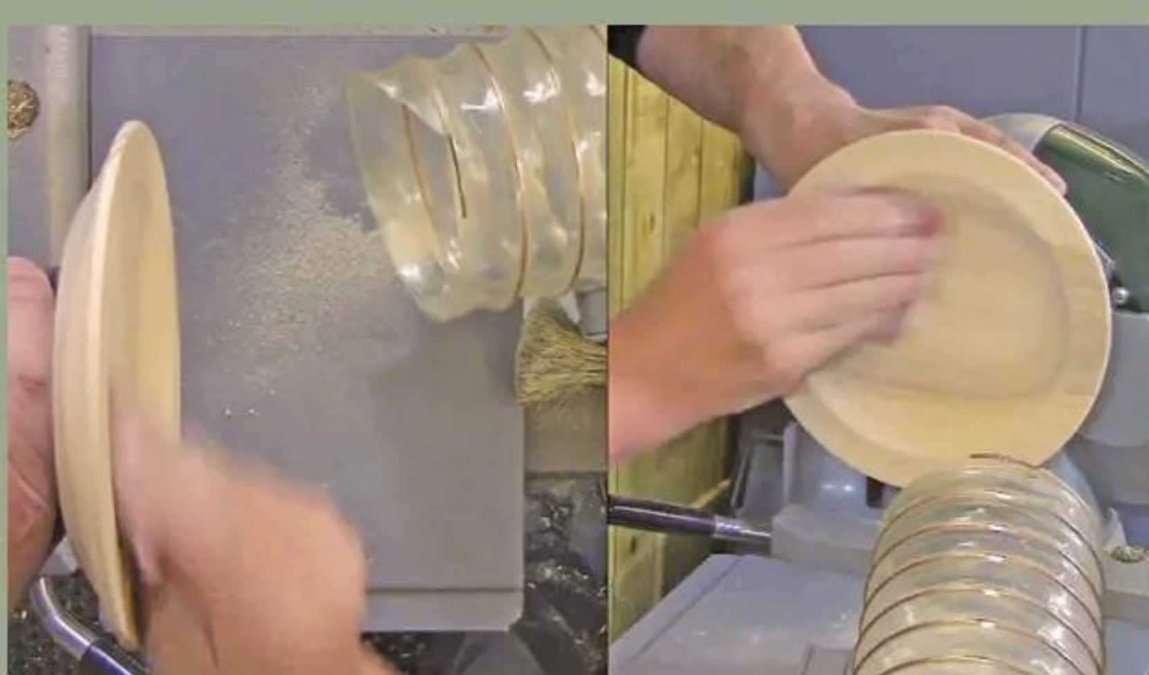
47 Sand through the grits to 240, again remembering to support the wrist and using all necessary safety equipment
