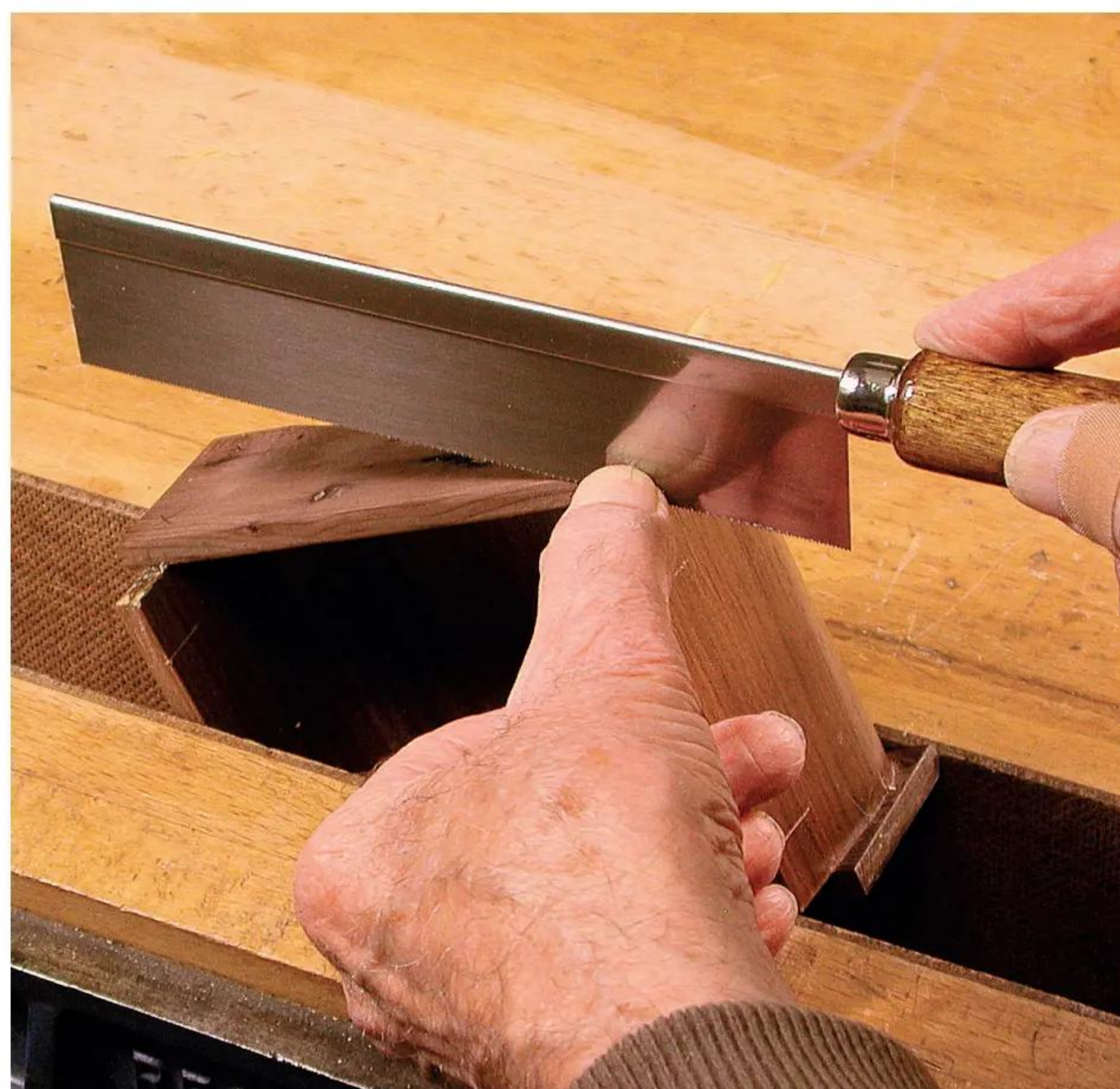
7 To cleanly cut thin stuff, I chose a very fine-toothed razor saw
