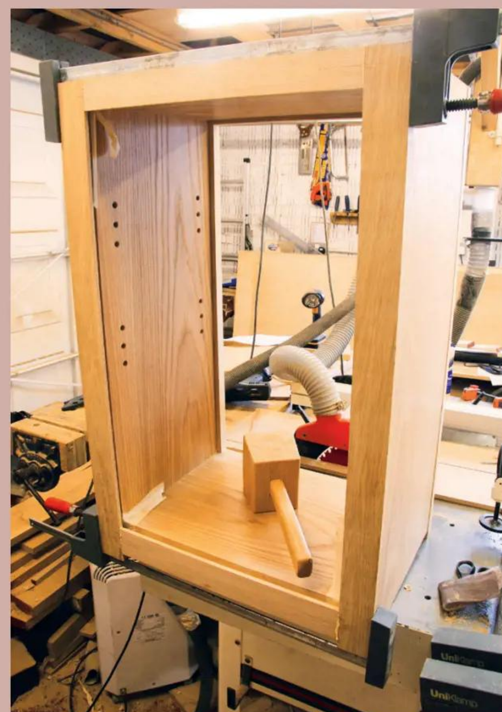
15 The frames were clamped up using the carcass as a guide
