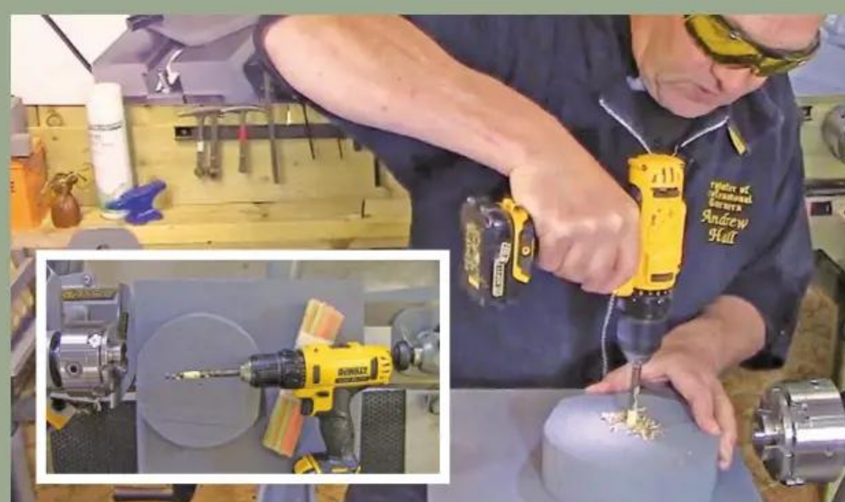
4 Most are 9mm, so I drill a 7mm hole with a cordless drill, the correct depth of the screw chuck, which will allow it to be screw mounted on the lathe
