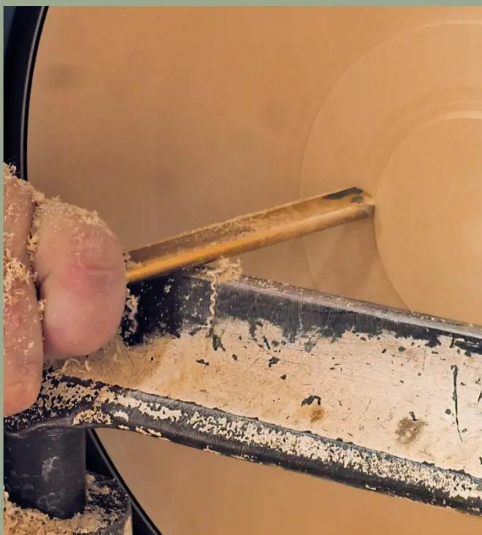
20 Provided I can get the toolrest close enough to the work, the smaller 6mm bowl gouge is my tool of choice for the final finishing cut, especially near the centre
