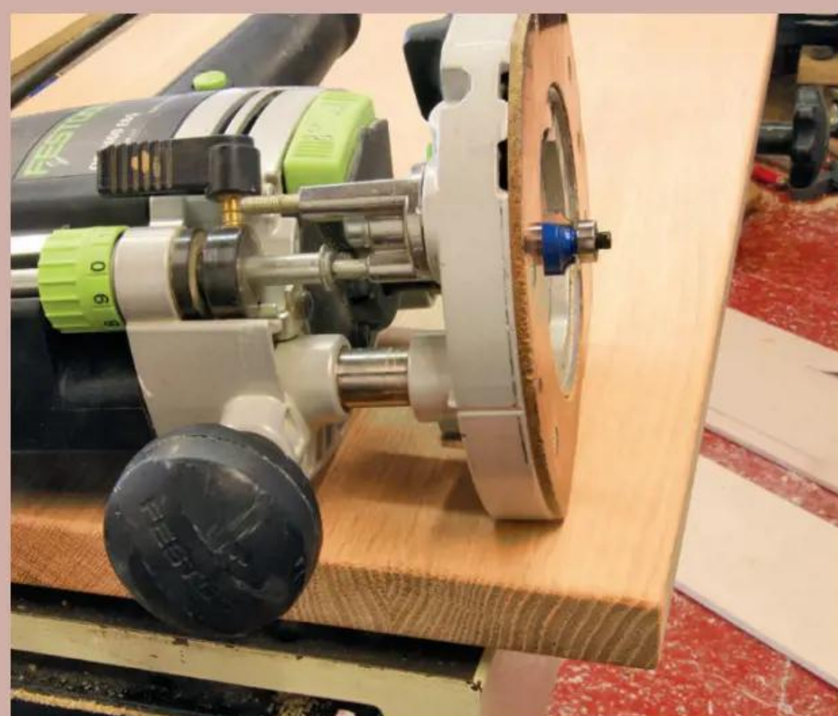
21 A 1/8in round-over bit was used to ease the top's corners
