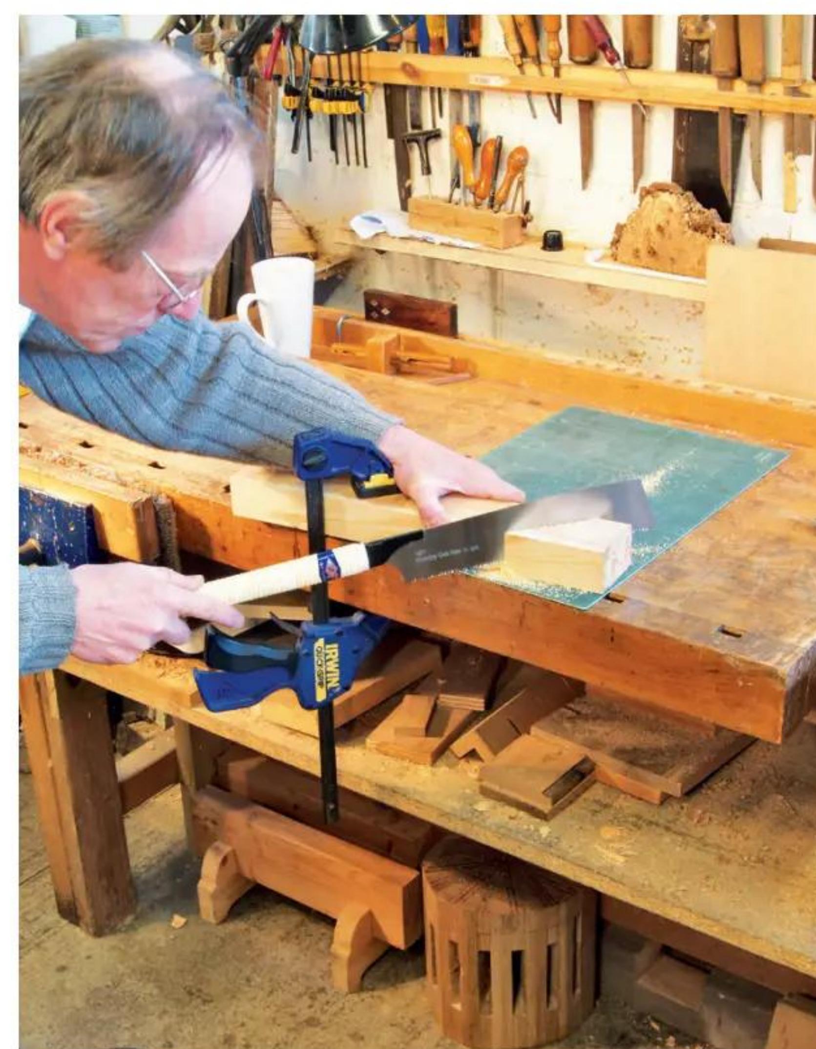
2 Cramp and saw to the line, ensuring your kerf is always in the waste
