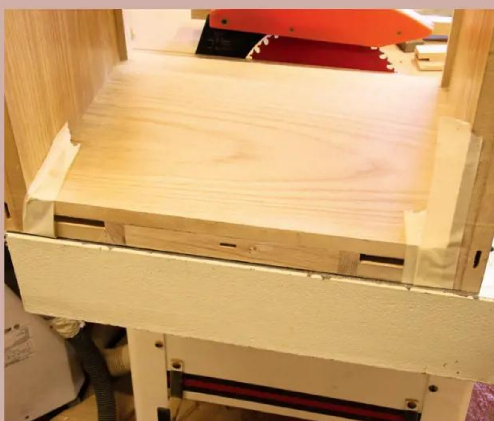
14 Masking tape protects the project carcass from excess glue
