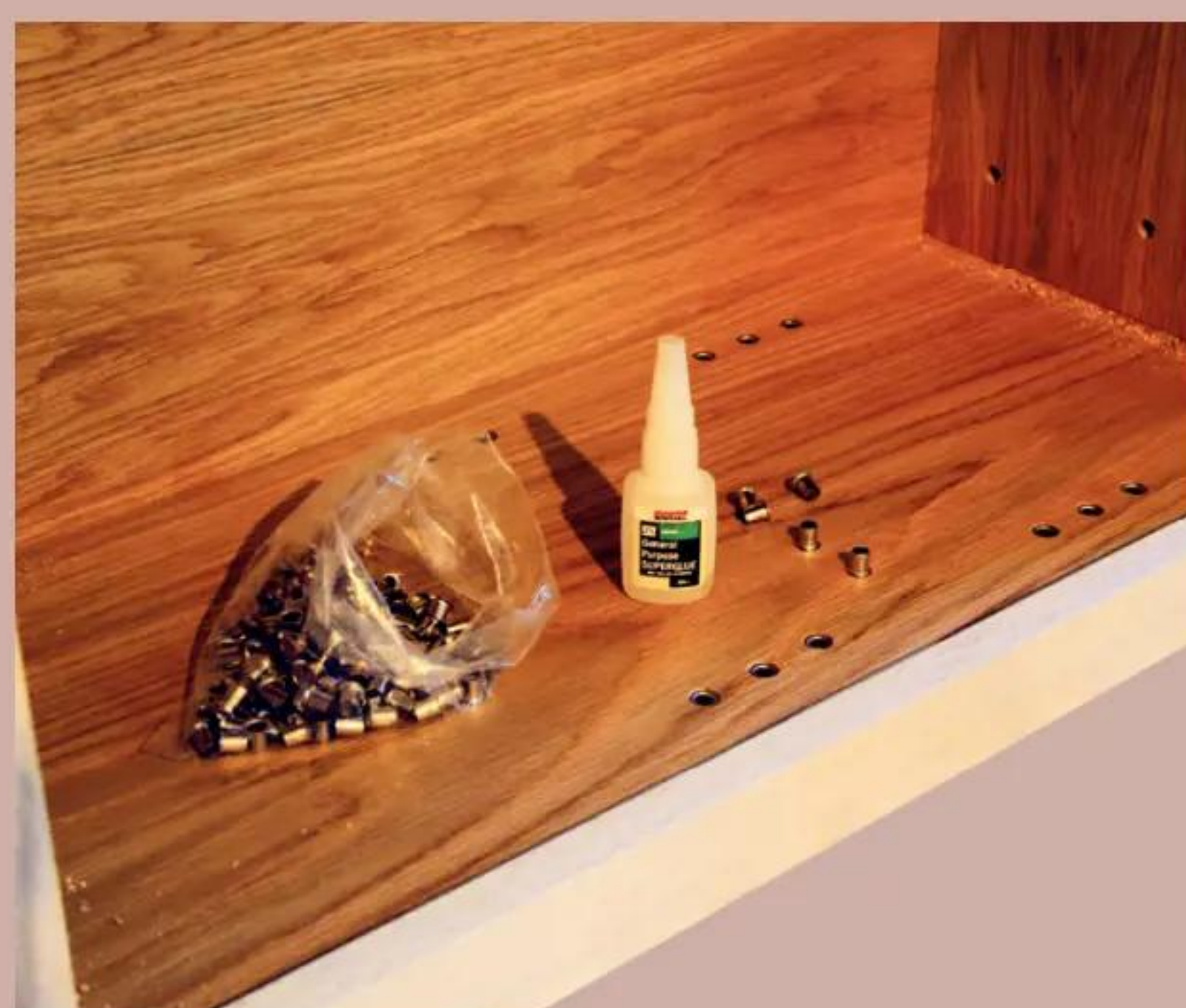
23 The shelf pin collars were glued in place with gloopy CA adhesive
