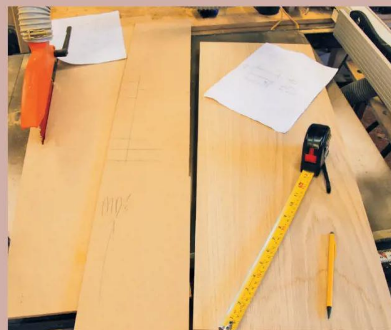
2 A rod was produced using the client's supplied measurements
