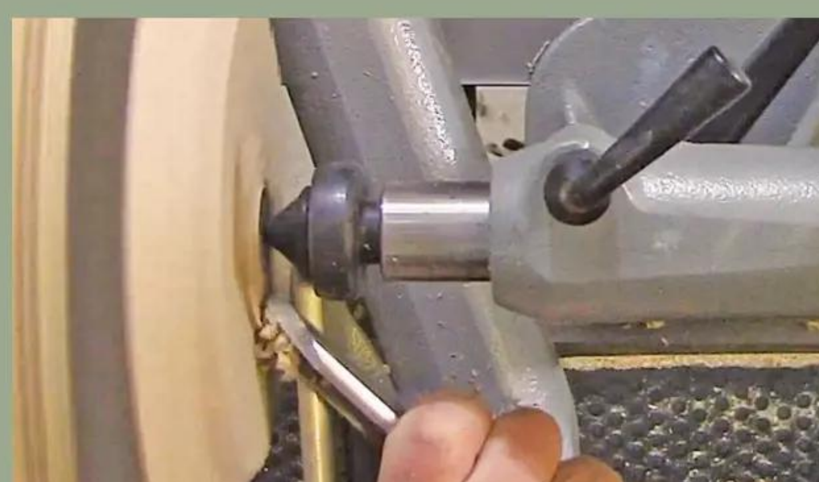
49 ... turn the spigot/tenon down to a 10mm dowel size using the swept-back bowl gouge
