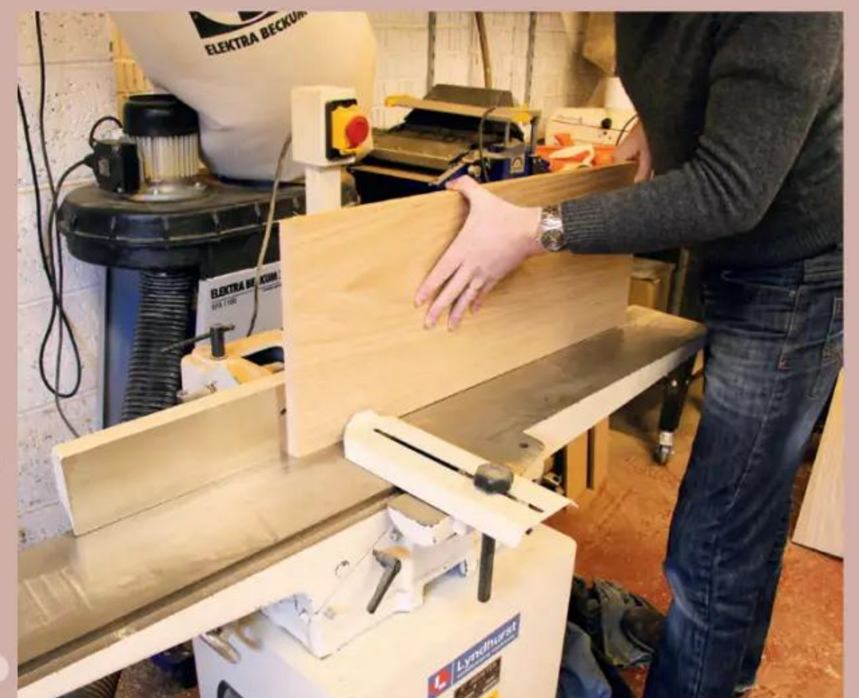
1 MDF can be planed in the same way as a solid wood panel
