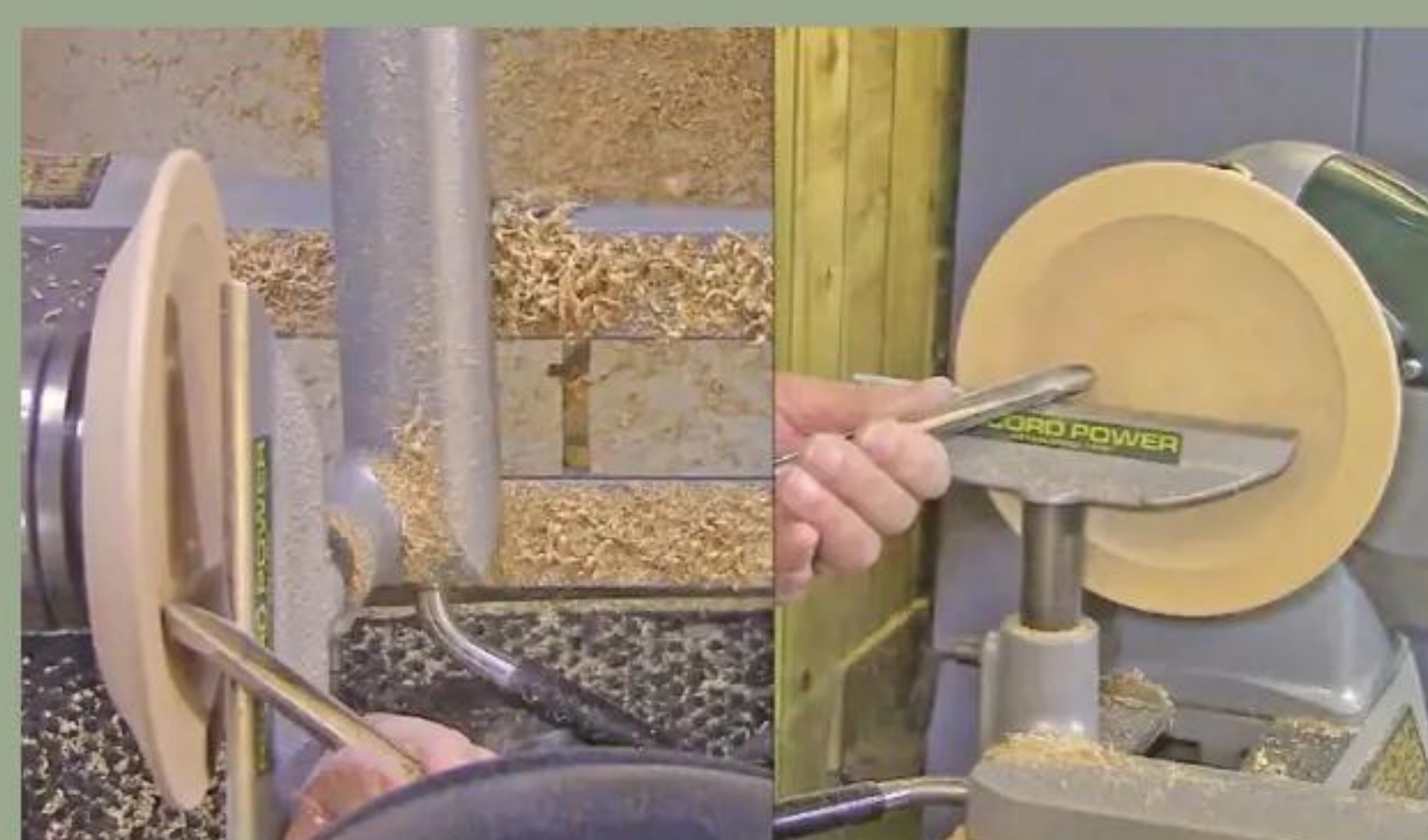
46 Using the same process as for the bowl, turn the centre to two-thirds the depth of the platter thickness
