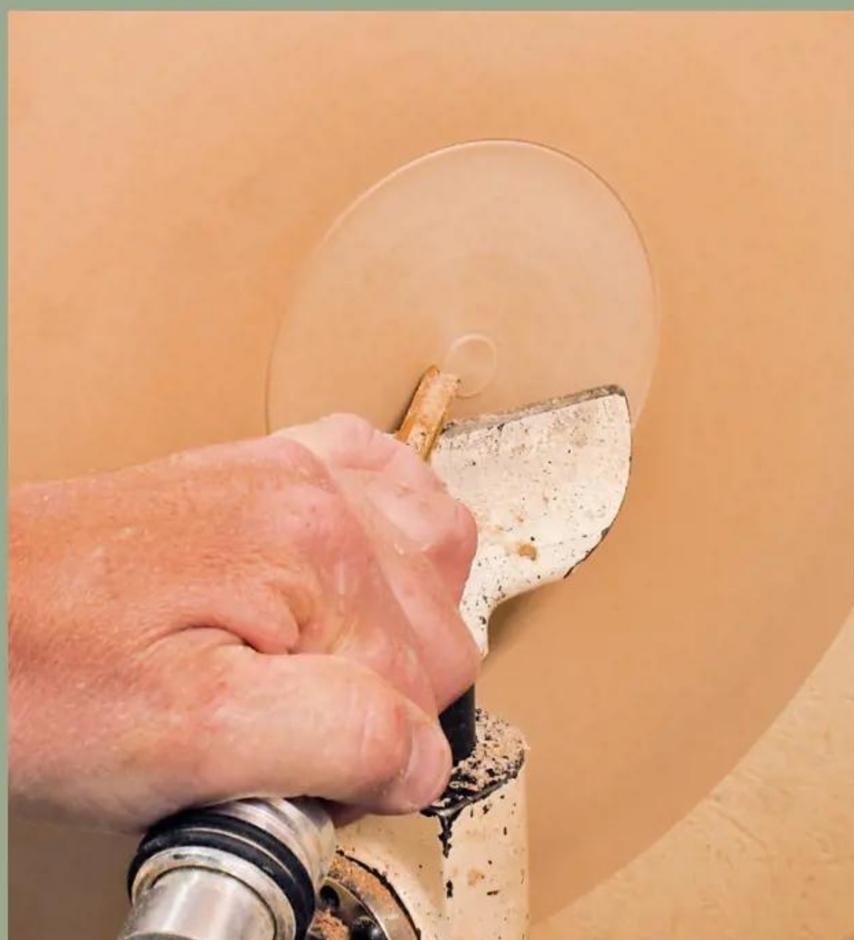
28 With the tailstock removed, finish off with light cuts into the centre, ensuring the base is slightly concave, then sand through the grades as normal
