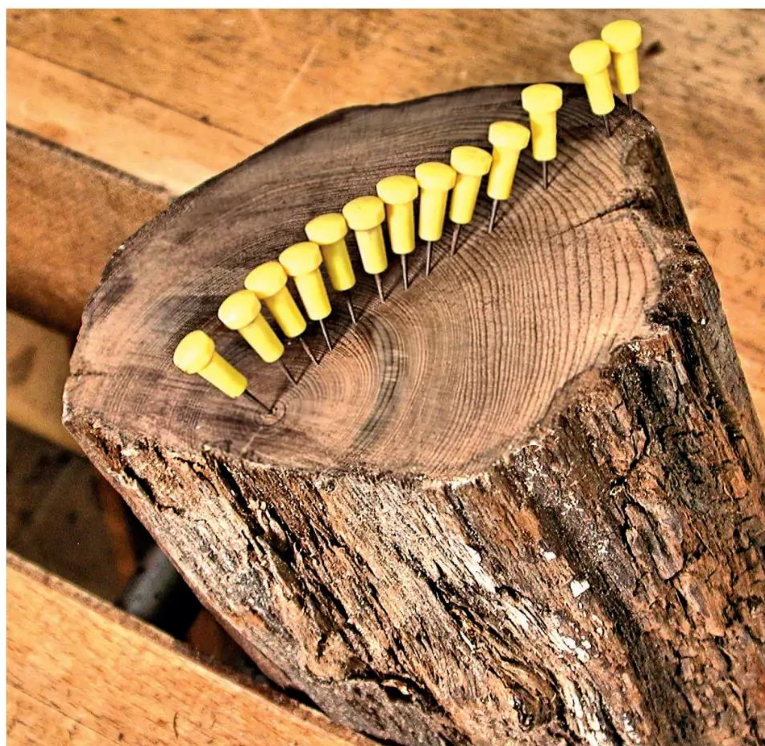
2 To keep track while counting, I marked each tenth growth ring with veneer pins
