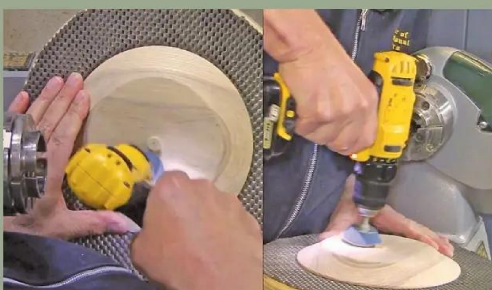
50 Using the sanding arbor in a cordless drill, sand the button to a flat surface on the platter's underside
