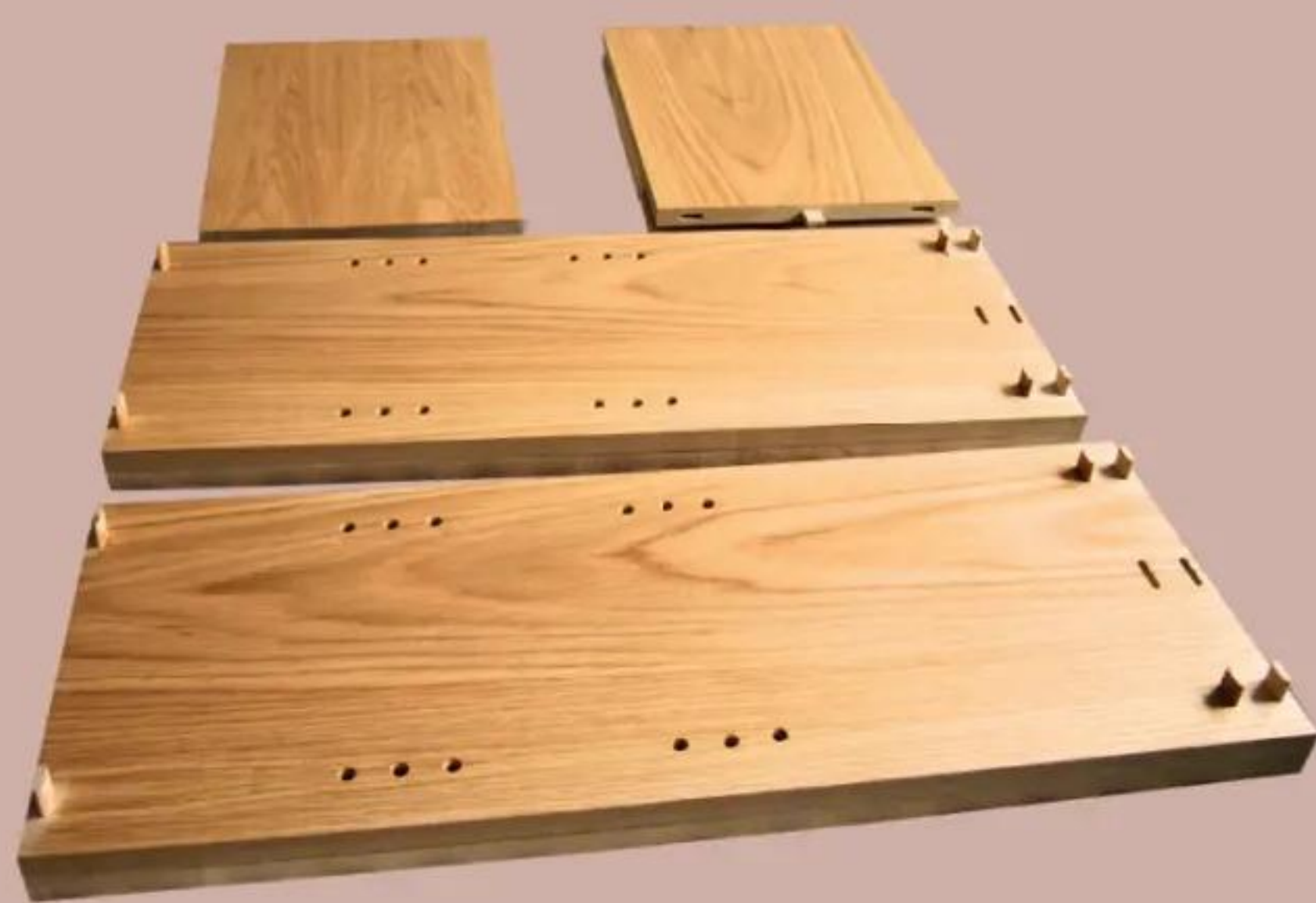
7 Before assembly, the internal faces were wax-oiled to give an easier finish
