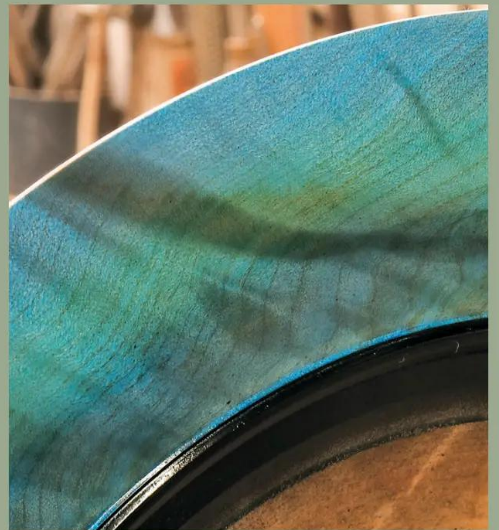
18 The edge close-up shows how the translucent stain penetrates the rippled timber at different rates to produce a range of shades
