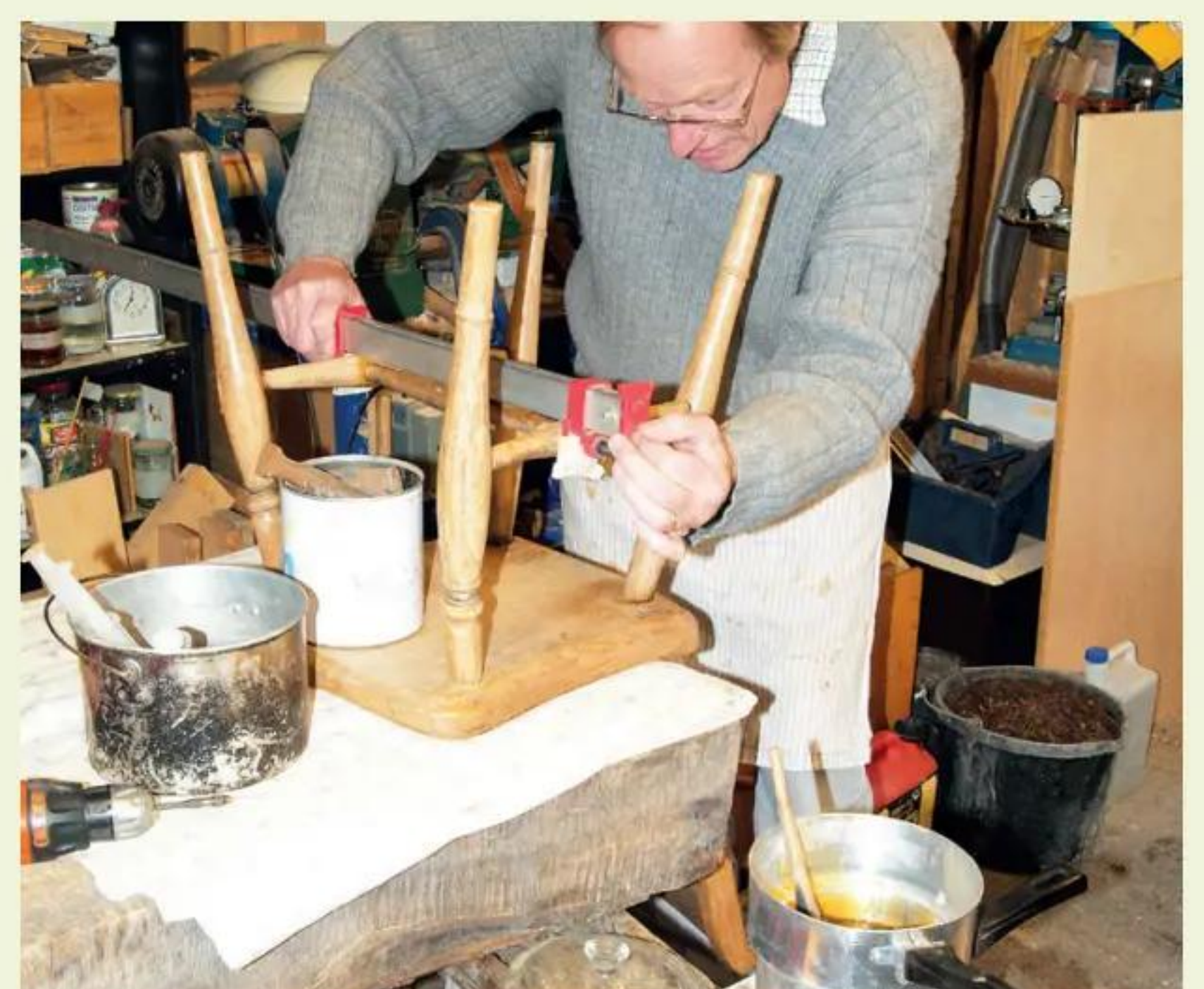
9 Finally, check everything is fully home; curing Scotch is quite tough, so it's not unusual to need a clamp to help the joints go home – not too much pressure, though! ✕
