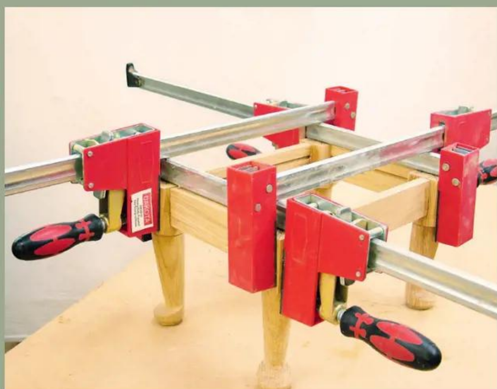
9 Next, glue and assemble all the joints, fit the cramps and test for square
