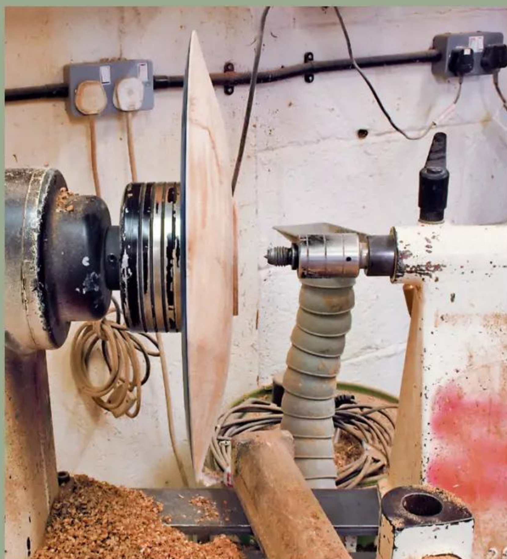
25 The bowl is sucked onto the 125mm drum chuck; now, barring power cuts and a huge dig-in with the tool, the work will stay on throughout the process
