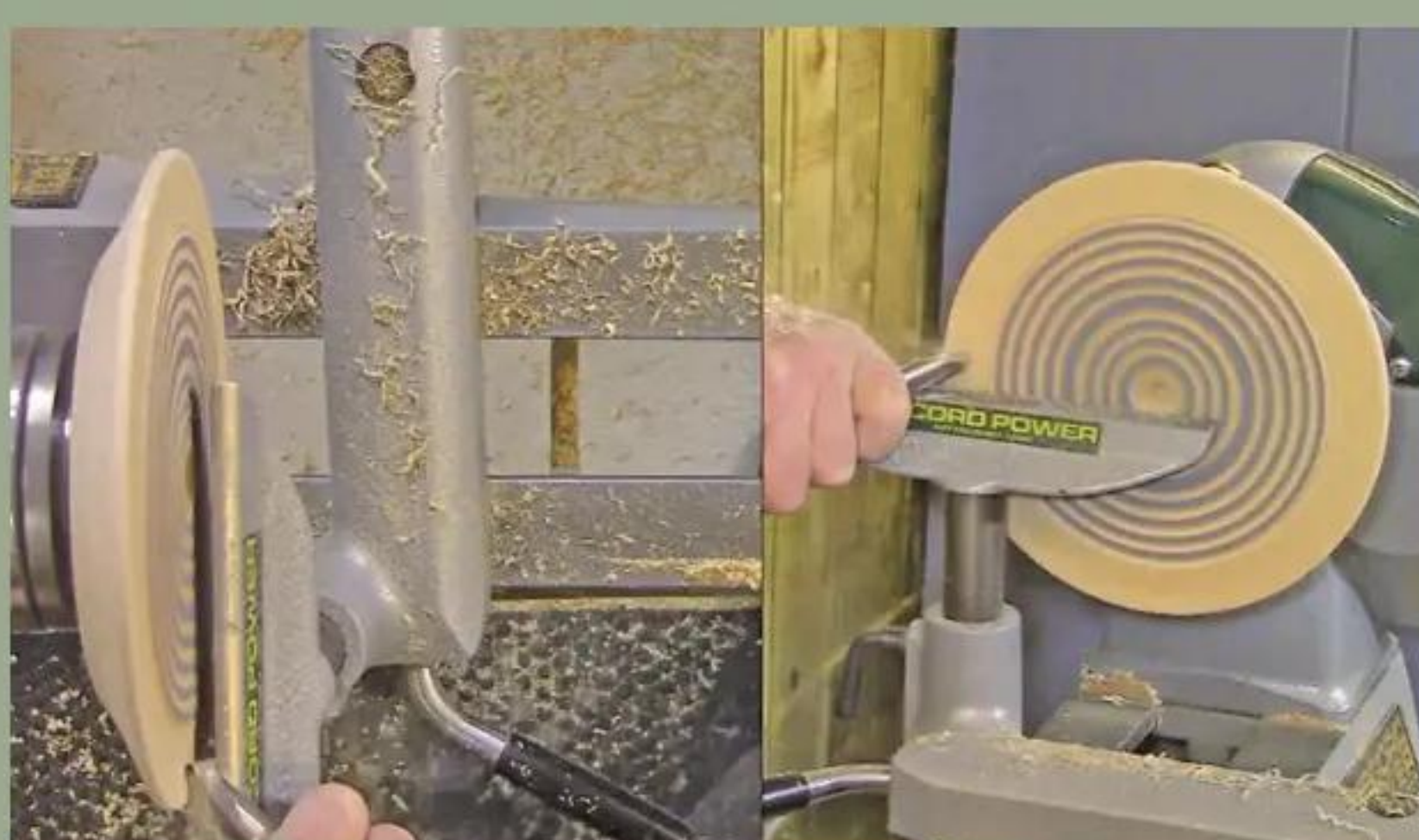
45 Clean up the edge with a draw cut down to a thickness of 6mm
