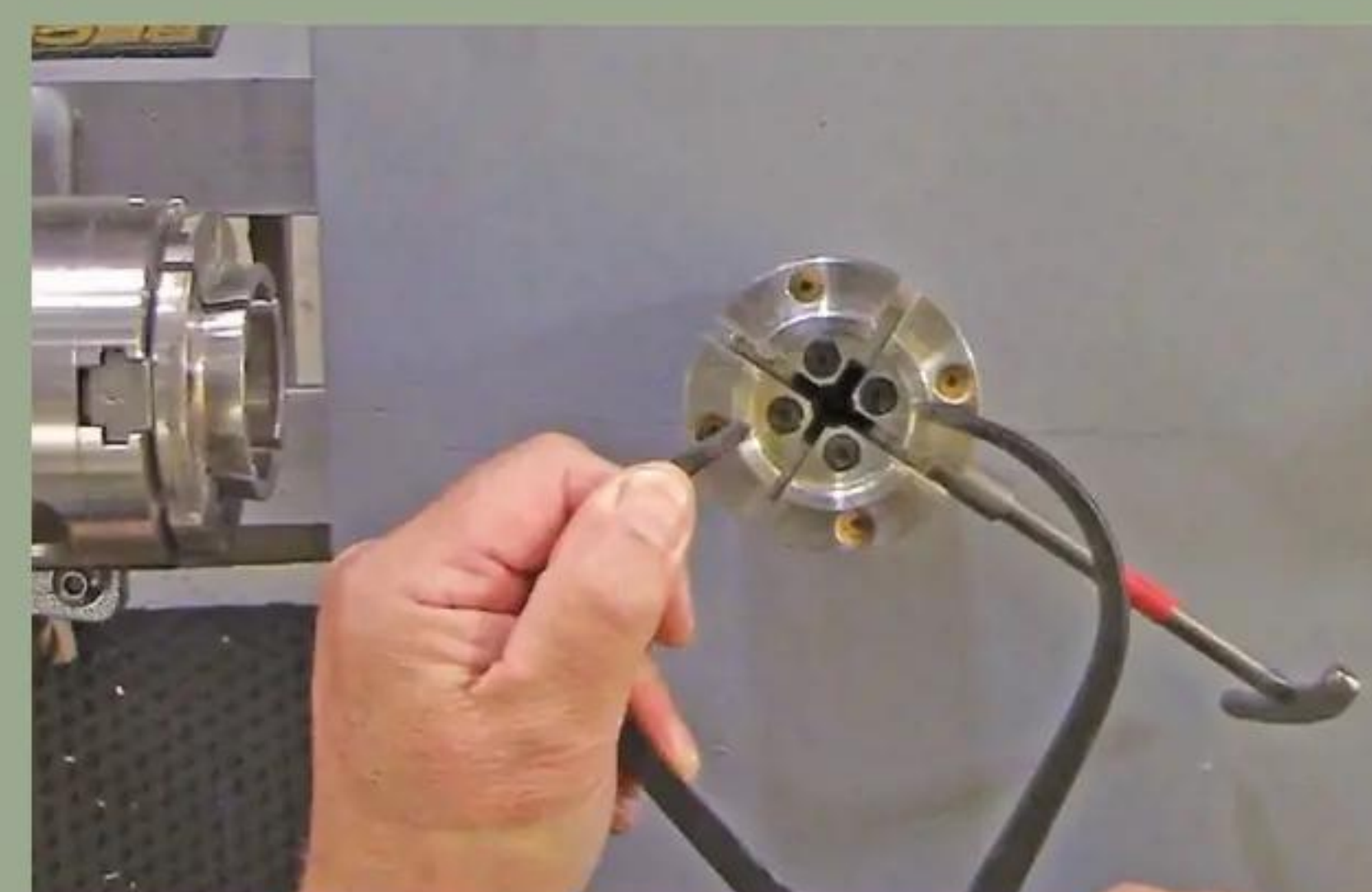
6 To gauge the spigot's size, I use callipers set to match the jaws' internal size...
