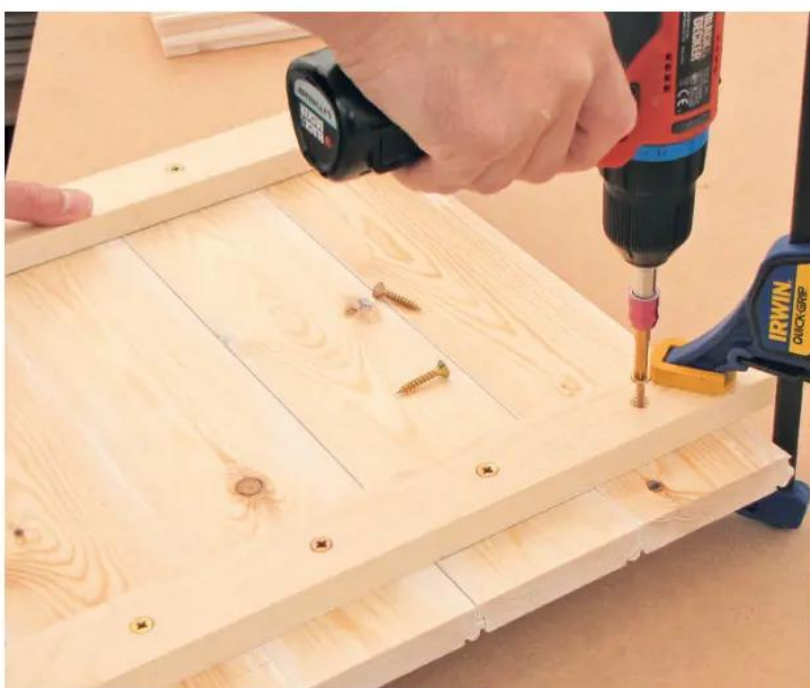
19 Screw through from battens into the boards; position the next board and repeat the fixing process
