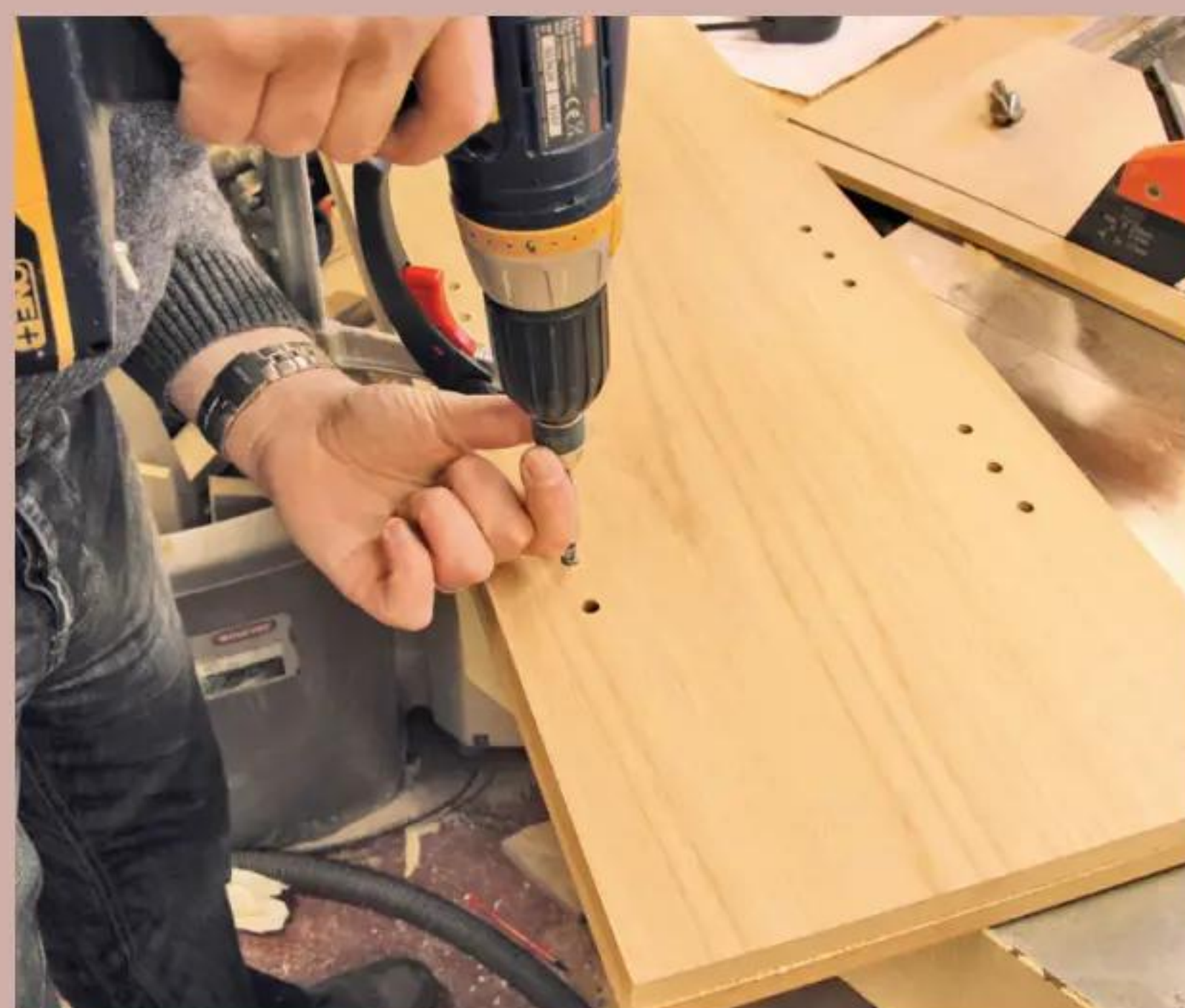
5 Pin holes hide screws that hold the doubled-up sides together
