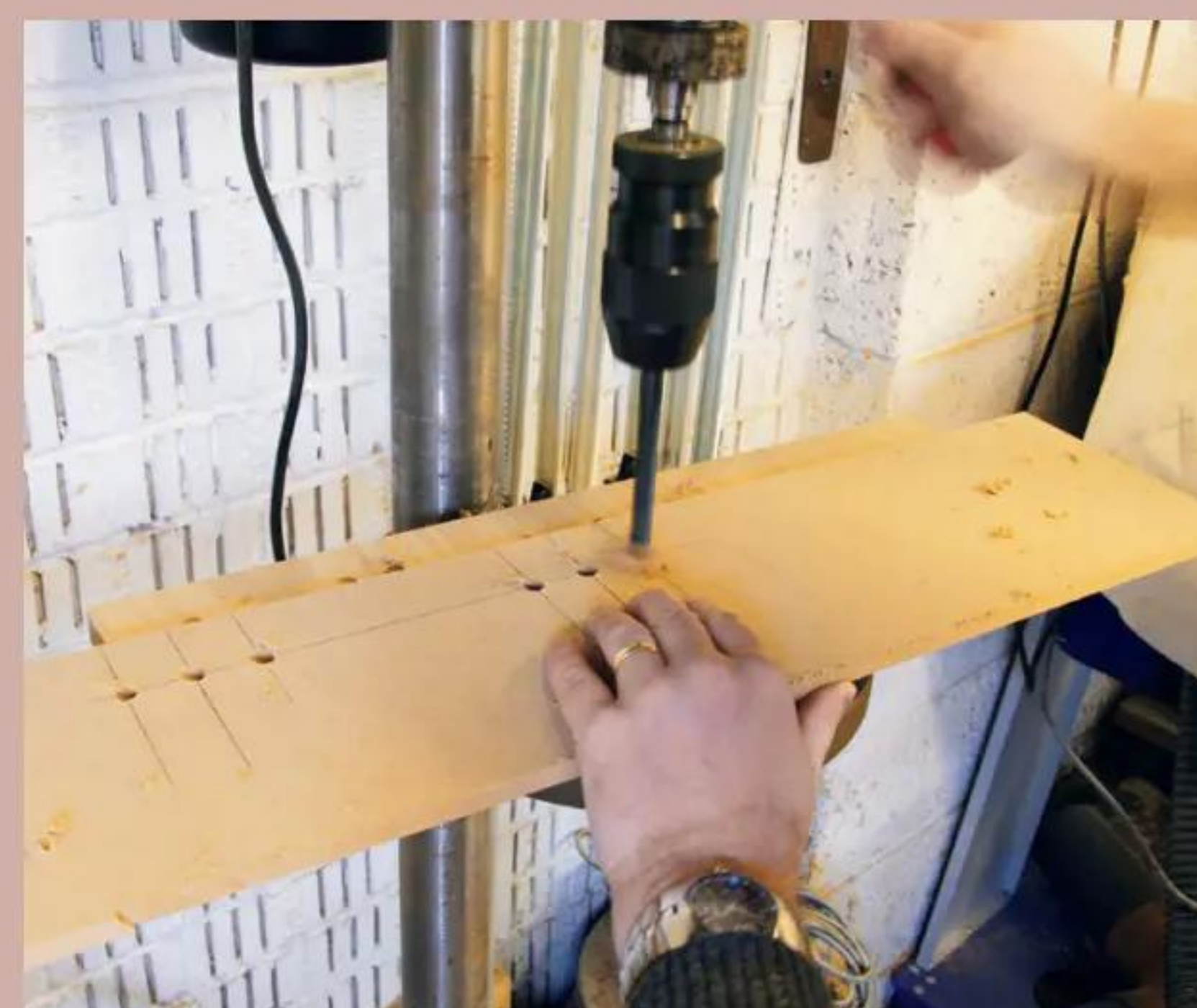
3 This was then drilled with the position of the shelf pin holes
