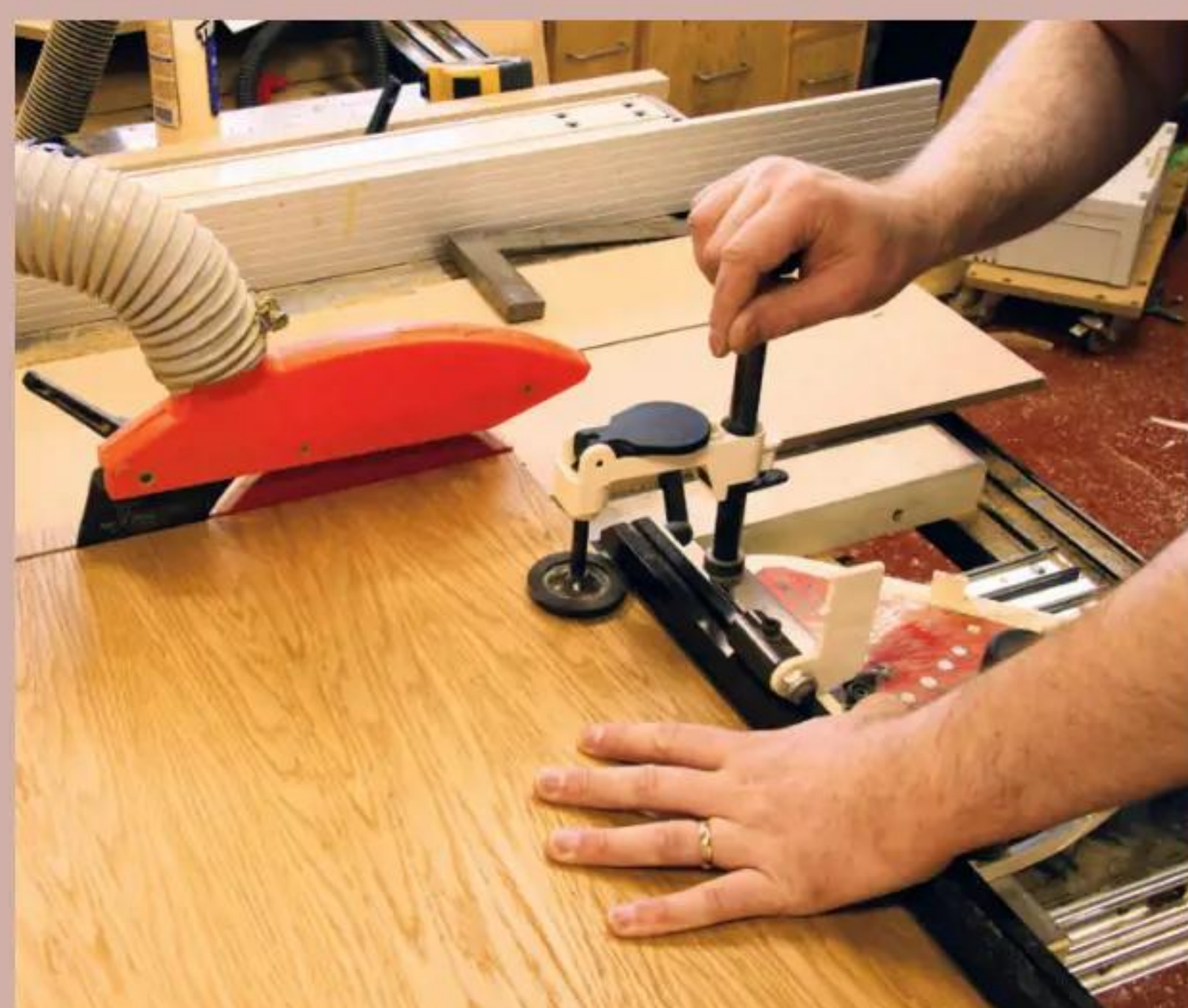
18 The rear panel was cut to size on the table saw. Note the temporary MDF top
