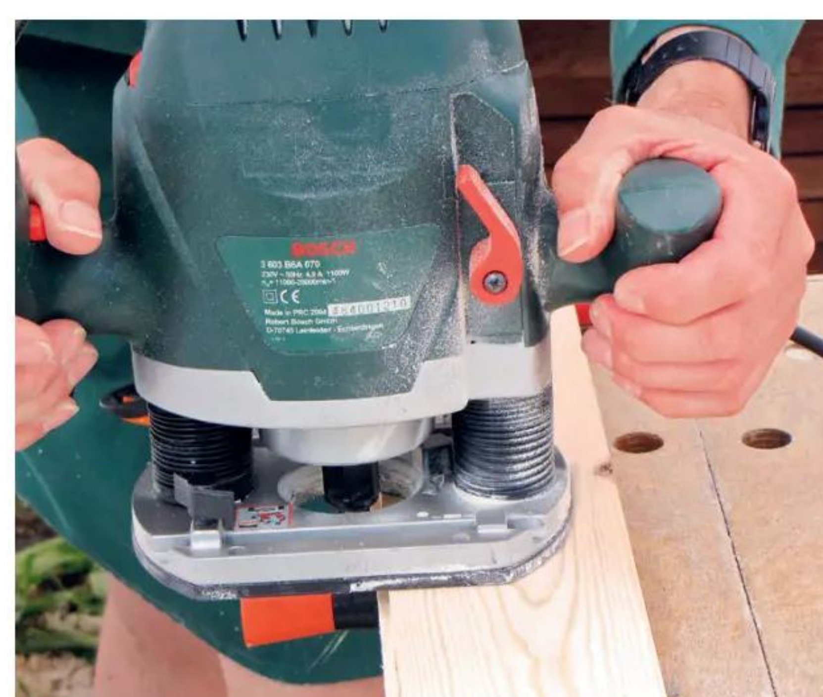
9 Rout a rebate on two of the edges to accommodate the beading tongue; sand boards prior to fixing
