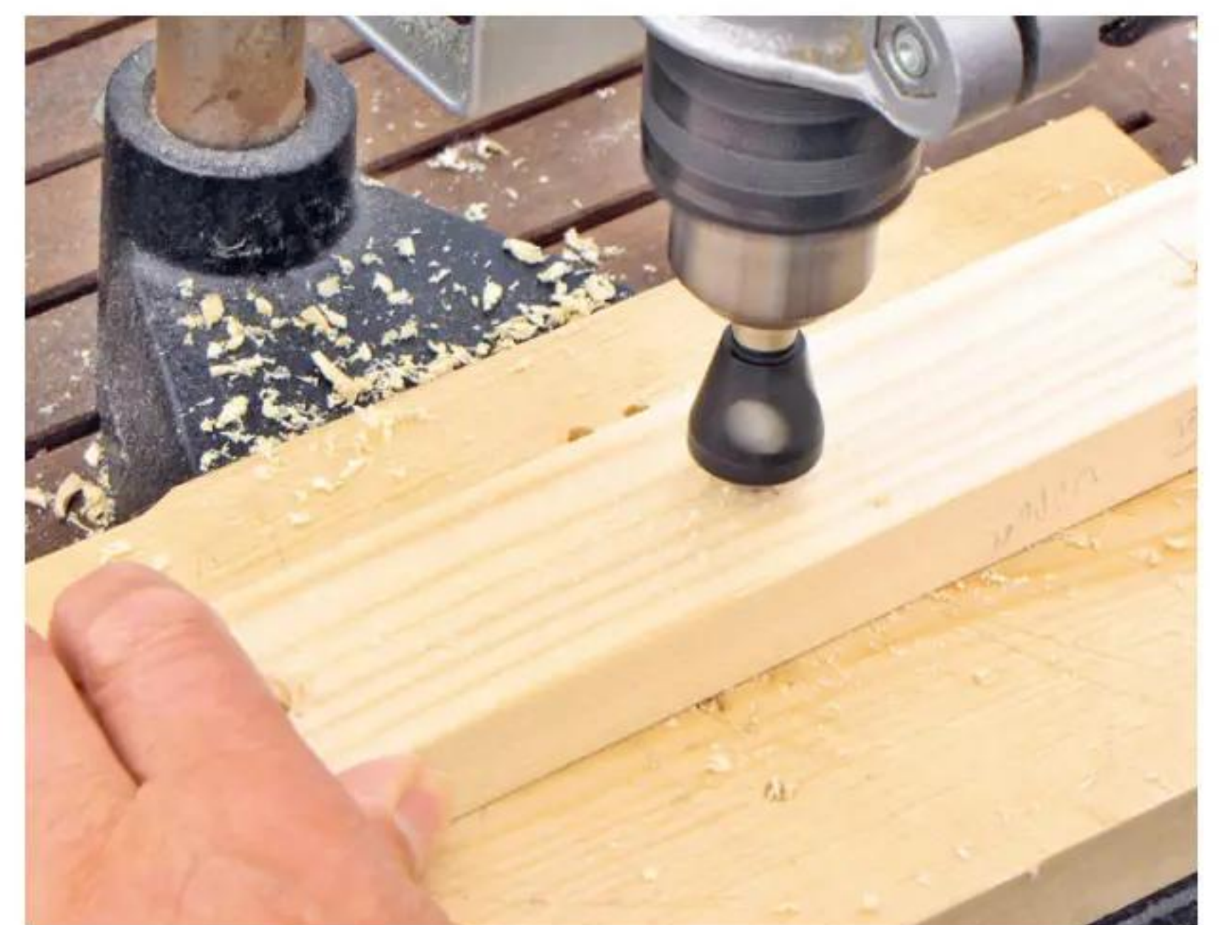
18 Drill and countersink the battens for 5mm screws; slightly oversize holes allow for movement
