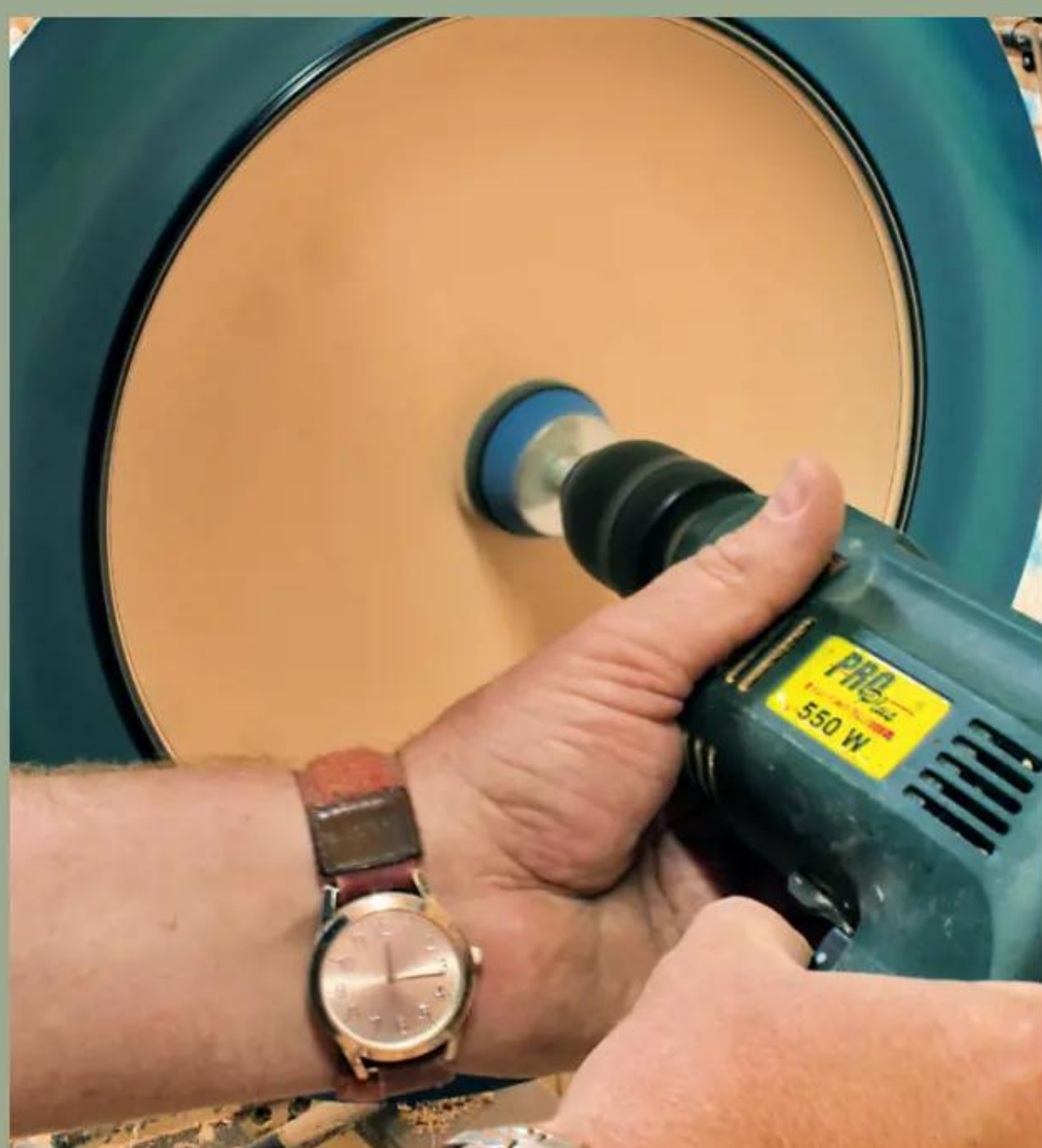
22 When sanding the platter interior, you have to be very careful not to run over the black rim. Ensure that the drill sanding pad passes over the bowl's centre so as not to end up with the dreaded lumpy bowl
