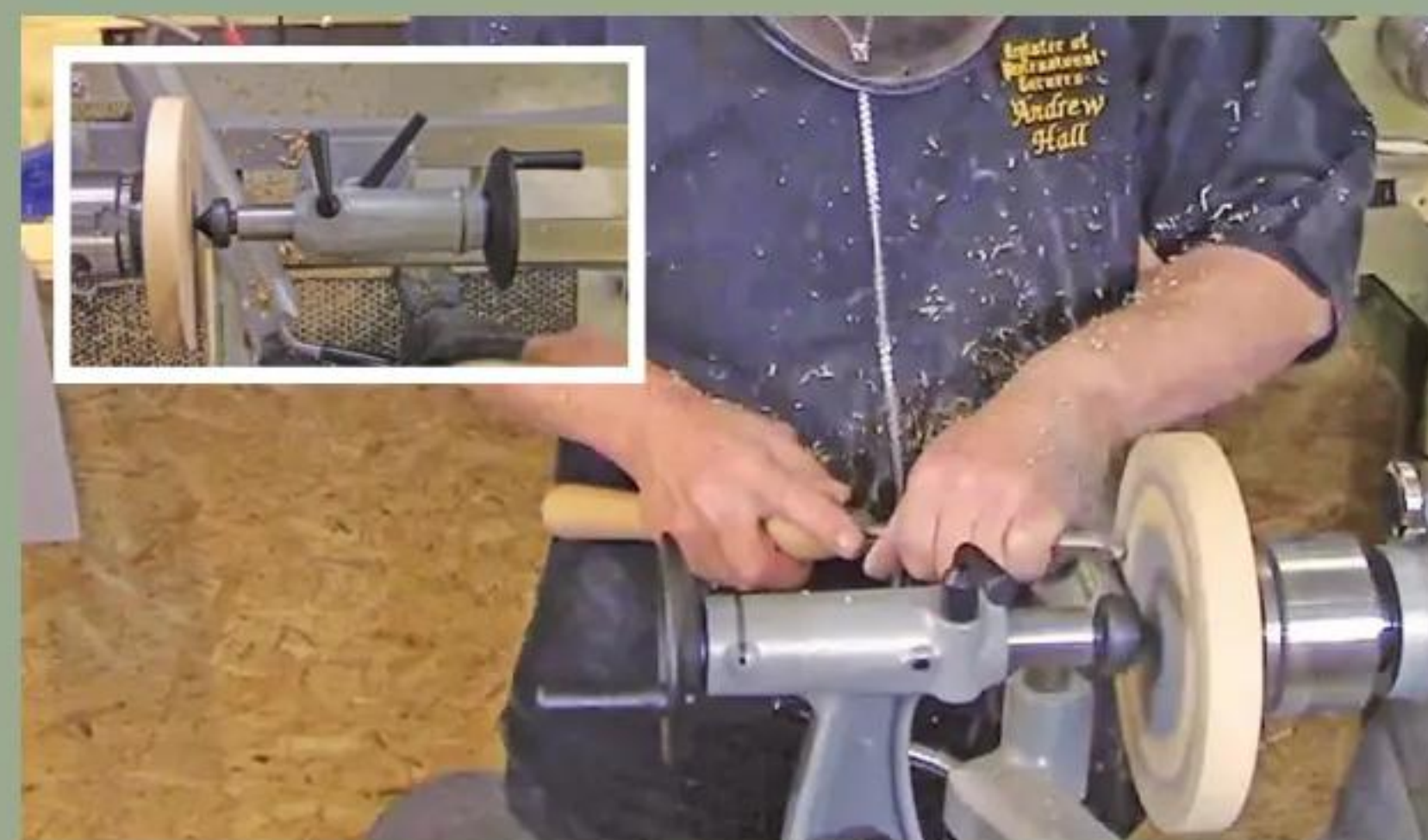
40 True up the platter blank's surface with a draw cut, leaving a pencil line for the spigot
