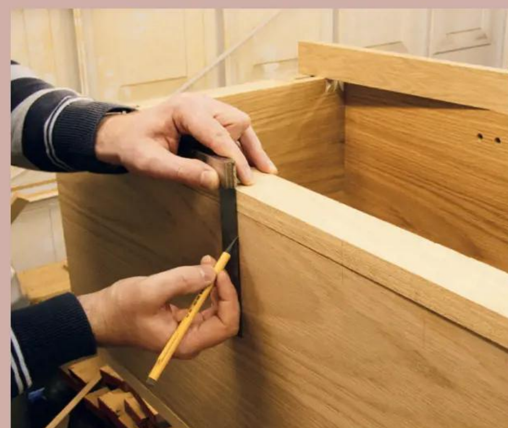
12 One Domino holds the sections in place while other slots are marked
