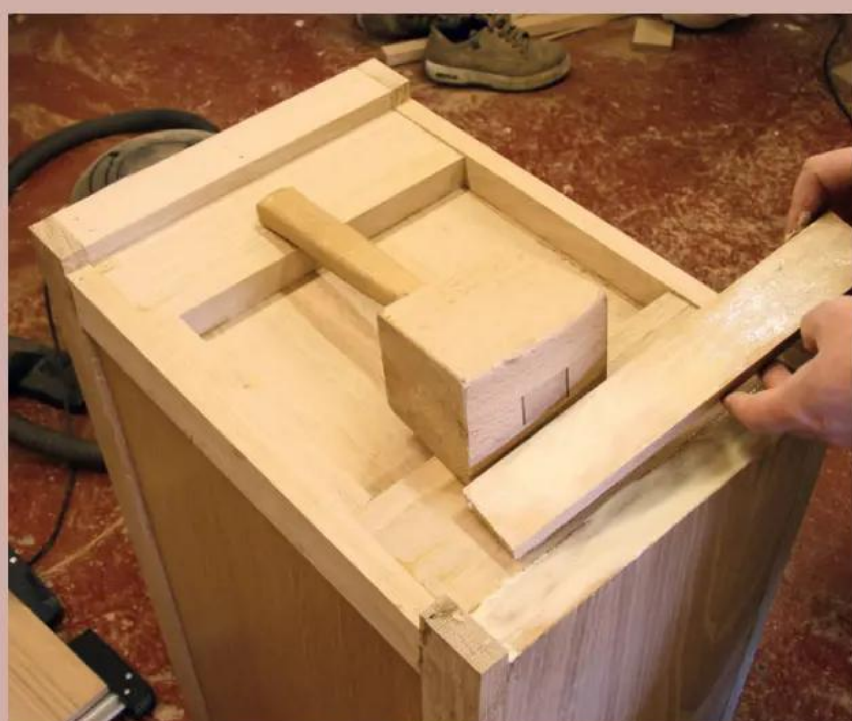
20 Leg sections connect front and rear frames, covering the MDF edge
