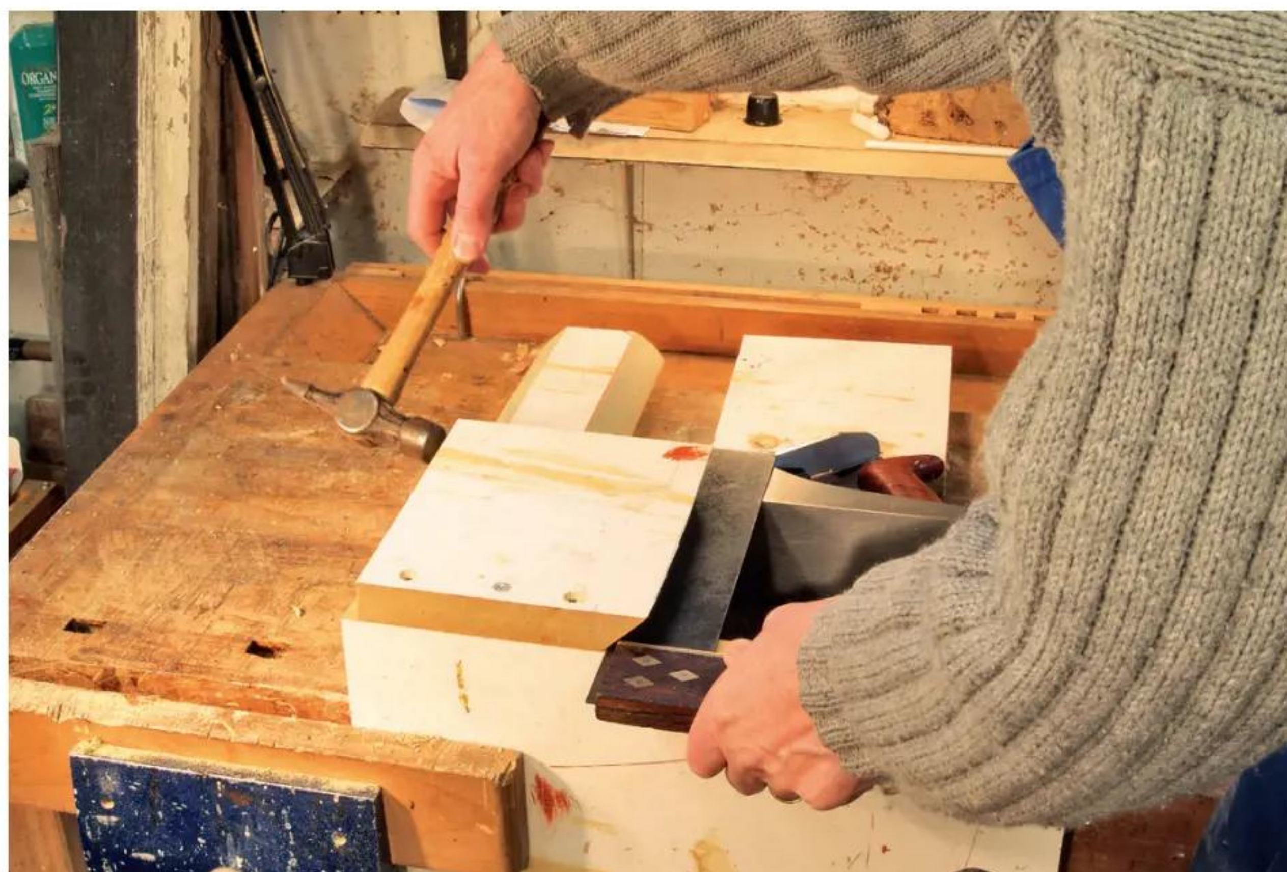
8 Fitting the mitre box's reverse. Ensure it's square; note the hammer. It's easier to locate a component by tapping gently as opposed to pushing
