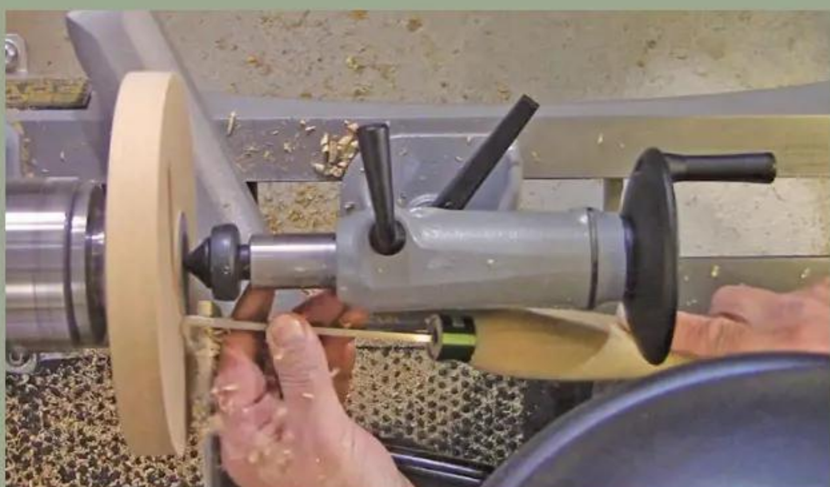
41 Using the 3mm parting tool, cut a spigot/tenon to match the chuck jaws' optimum size, creating a slight dovetail; this will allow you to achieve 360° of contact
