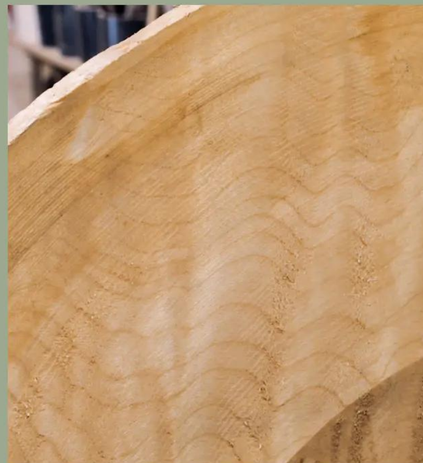
3 Just what I needed: to obtain the best effect from the staining, you need to have some ripple or figuring in the grain; if there wasn't any curly grain in this blank, I'd select another
