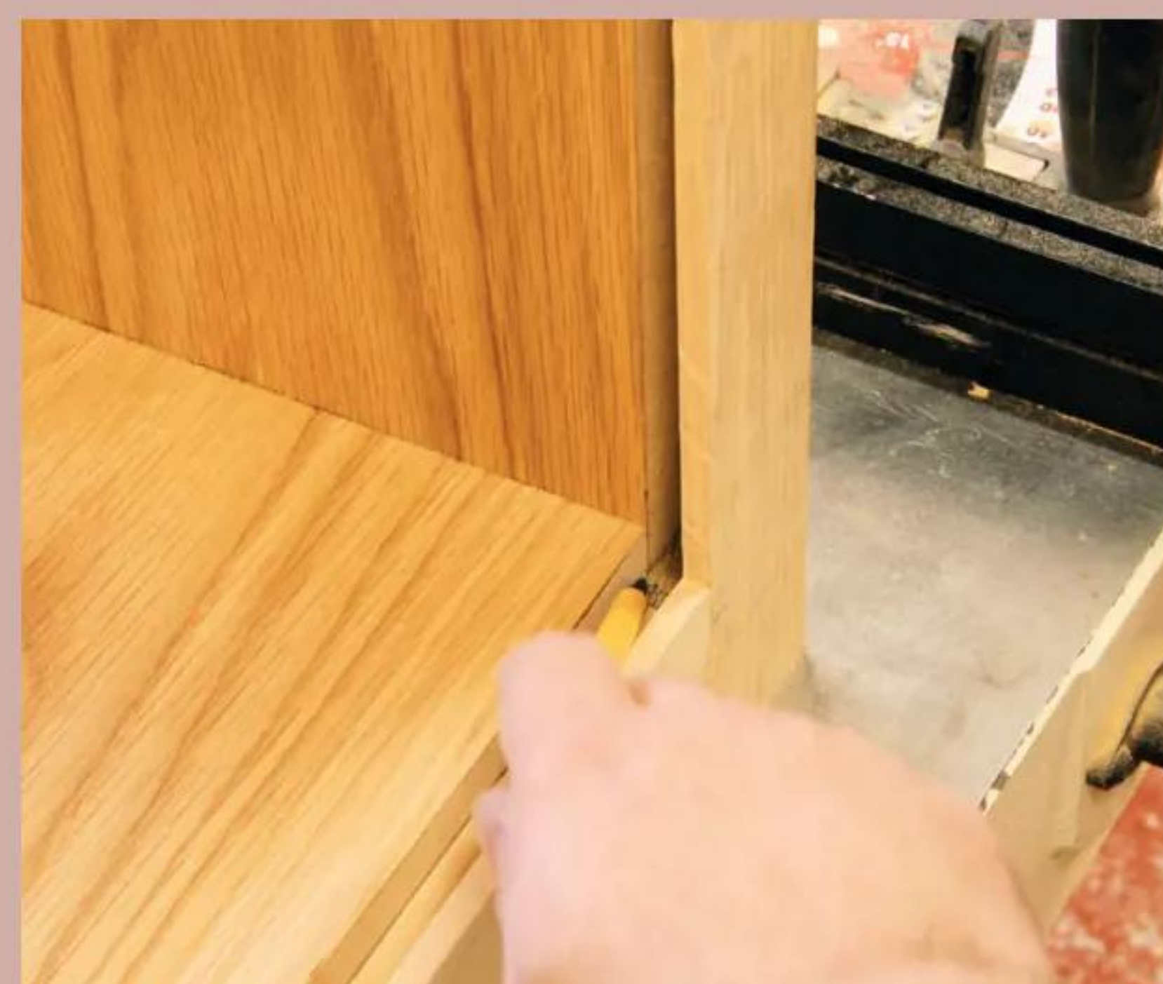
17 With dry-fitting, a pencil line gives accurate dimensions for the rear panel
