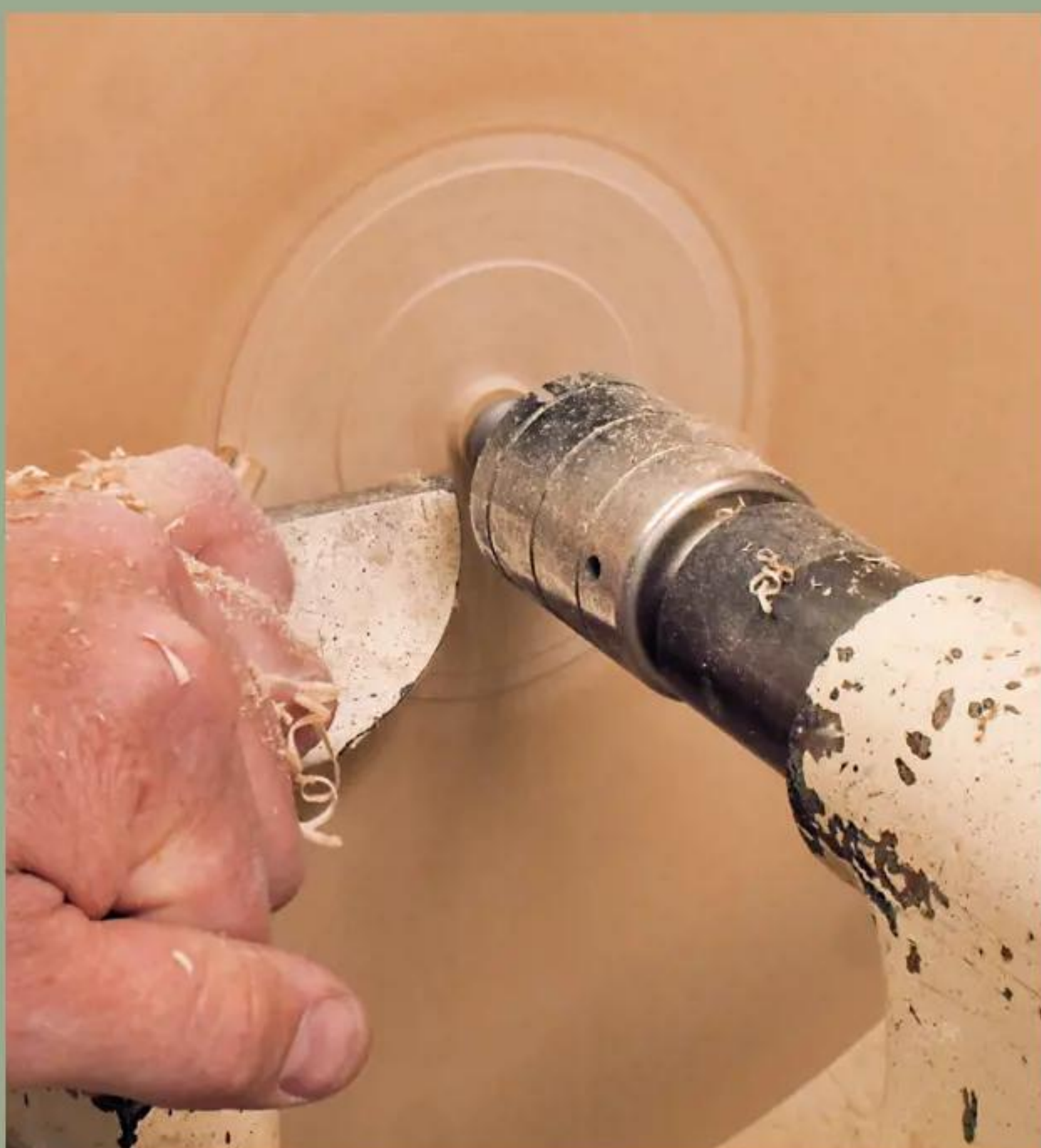
26 At this stage, light cuts with a small tool are the order of the day. I've put the tailstock centre back in place for added security and proceed to take light but positive cuts
