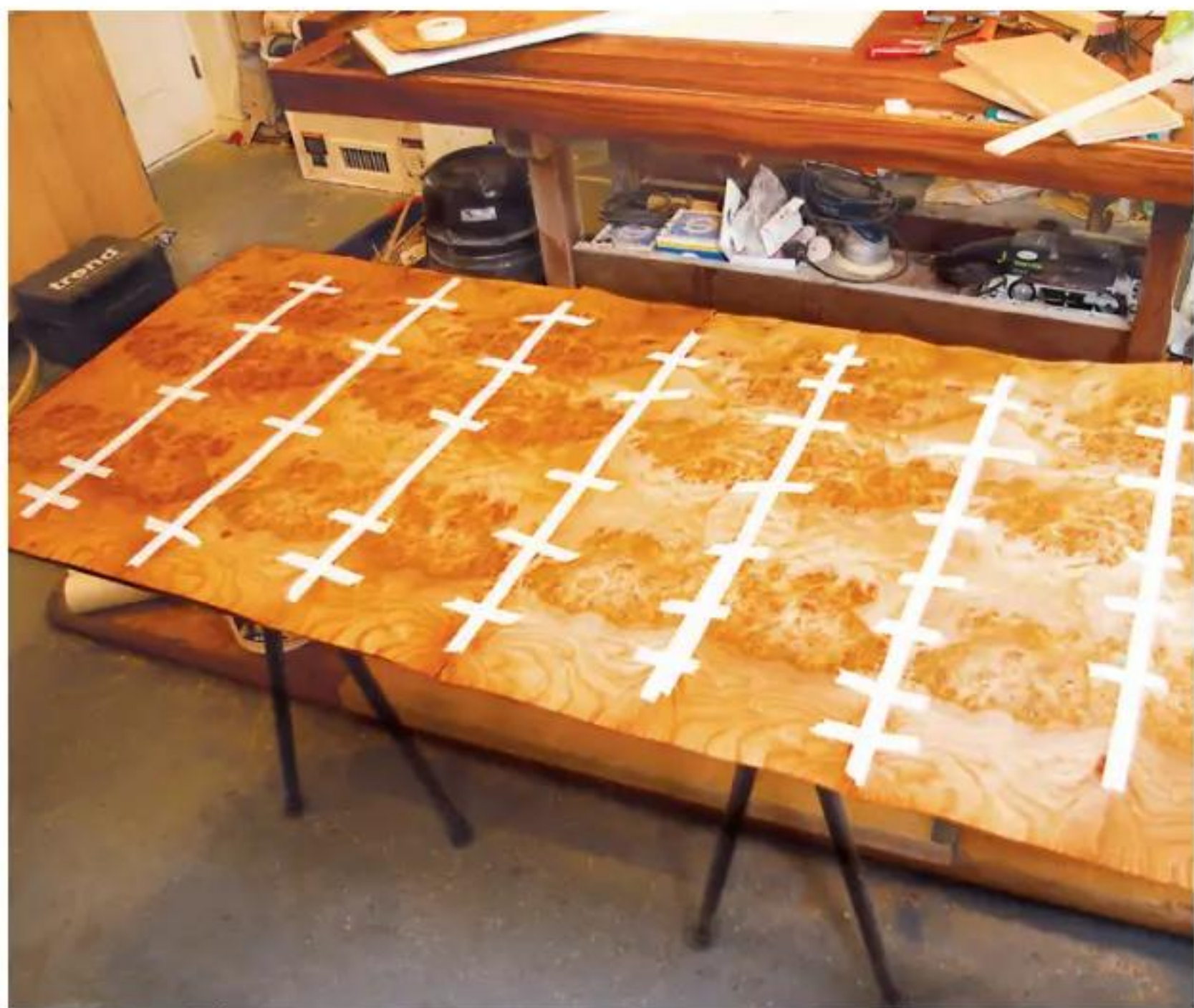
22 The veneer for the top, which forms the top of the shelf, is made up by shooting and taping together separate leaves
