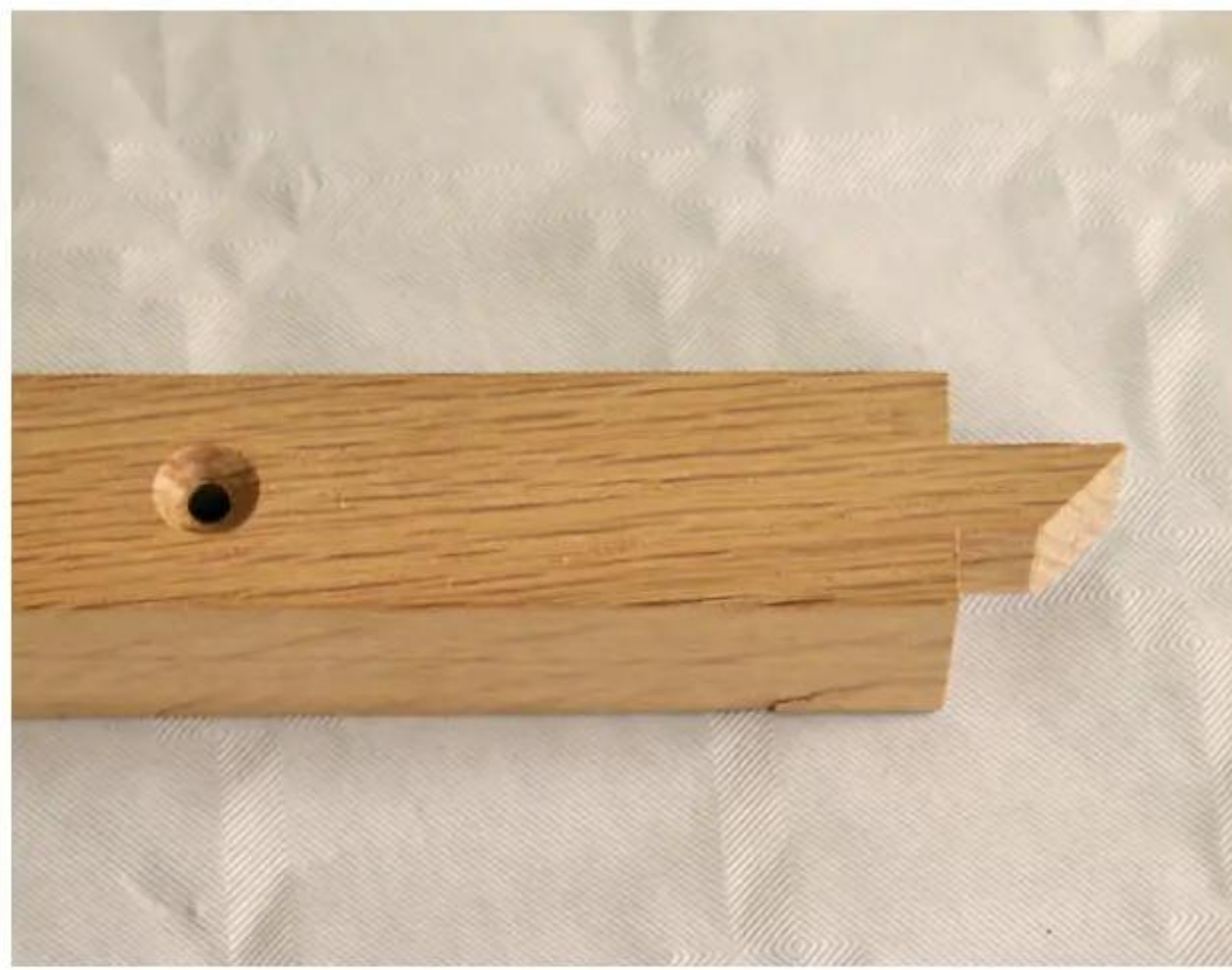
8 I glued and screwed the four top cross-pieces to the lantern's top by means of screws, which were inserted half way along their length. It's best to drill and countersink clearance holes for these prior to assembly
