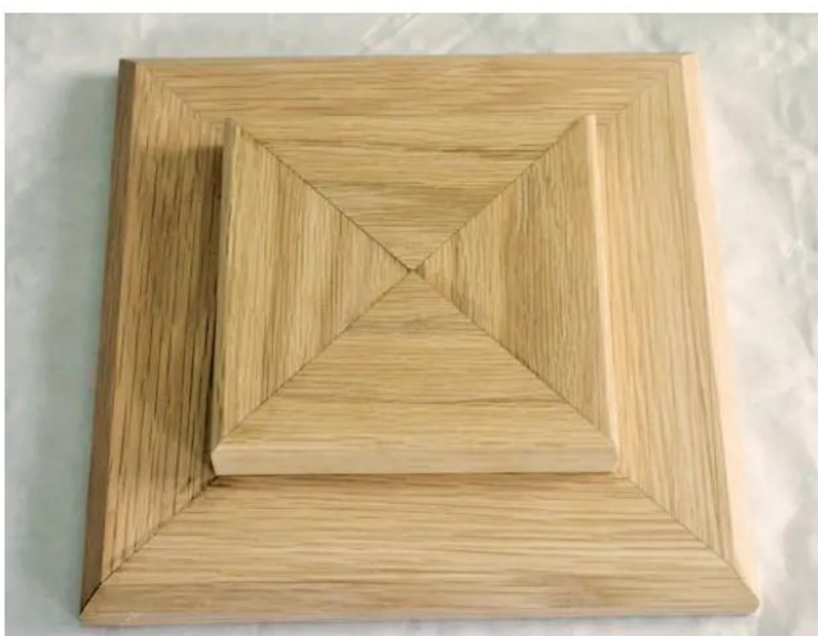
13 To assemble the top, I applied minimal glue to the cap piece and centred it, then rubbed the two components together until they both sat tightly in the correct position
