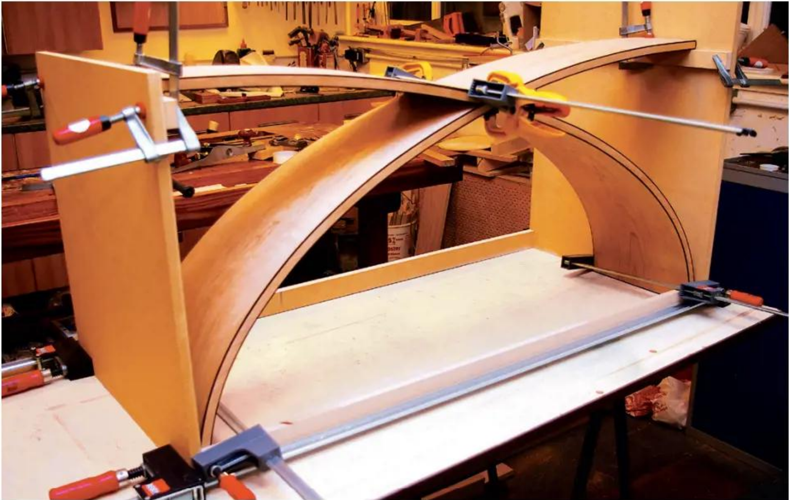
21 With the legs complete, assembly can take place
