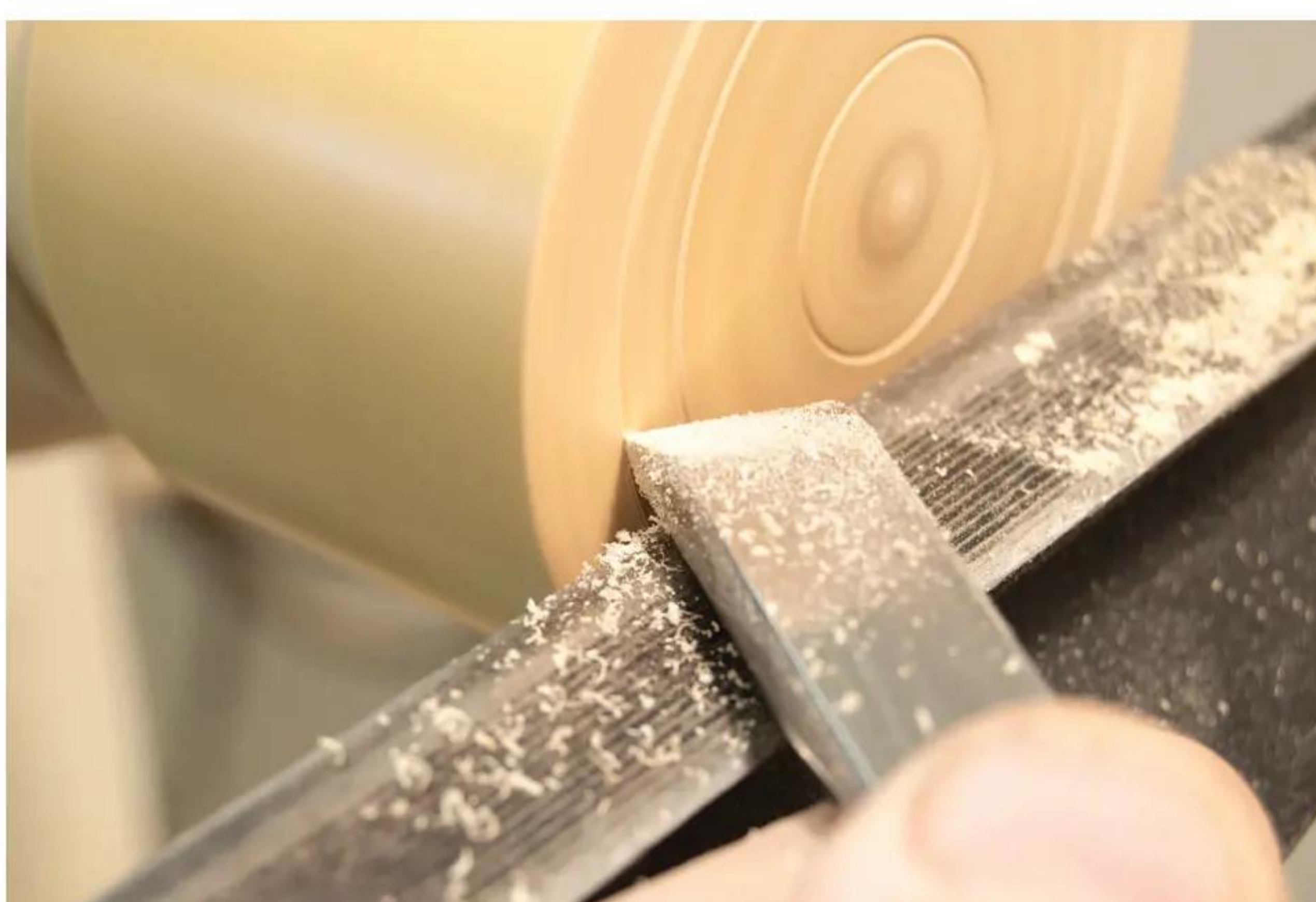
18 Using the point of a skew as a scraper, make some decorative grooves...
