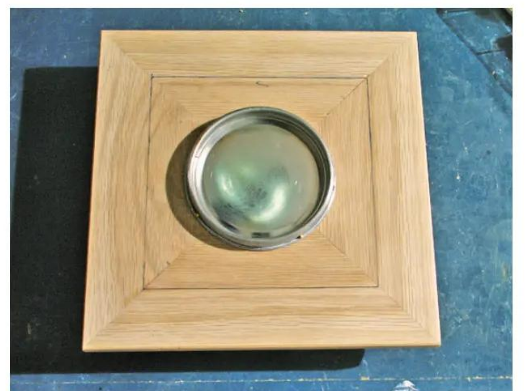
15 Pinning a paint tin lid in place with brass pins produced an air gap between both the oak and heated metal
