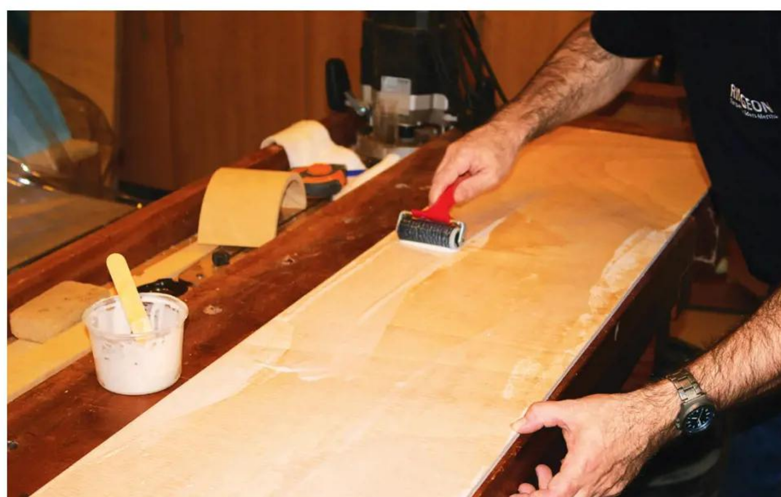
6 Glue up the sheets of bendy ply using Cascamite and a roller...
