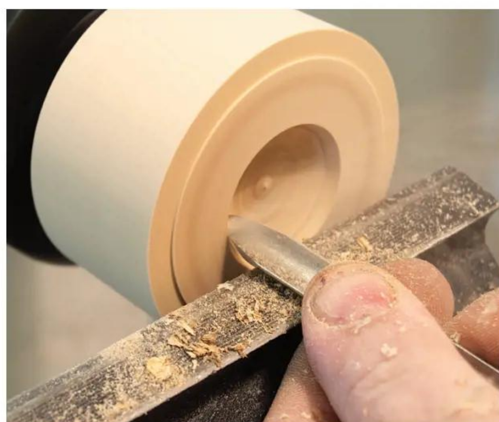
5 To begin the hollowing process, present the flute at 10 o'clock with your right hand slightly lowered
