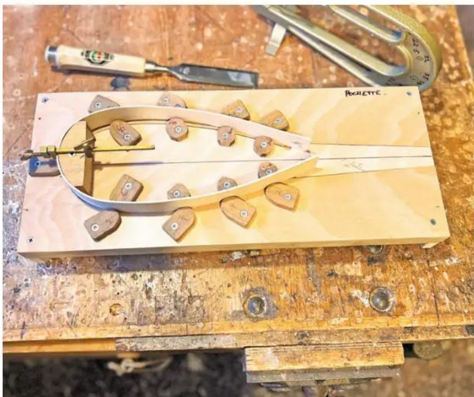
10 Sides – ribs – held in place with work board cams
