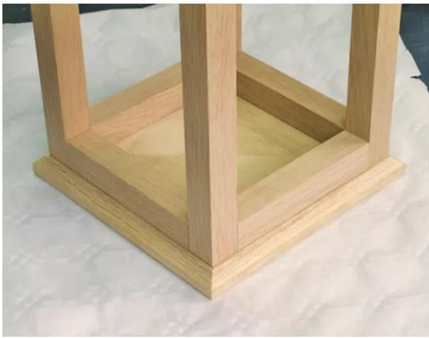
17 To complete the lantern assembly, I glued the framework to the base section, using the previously made markings, and applied four screws once the glue had set
