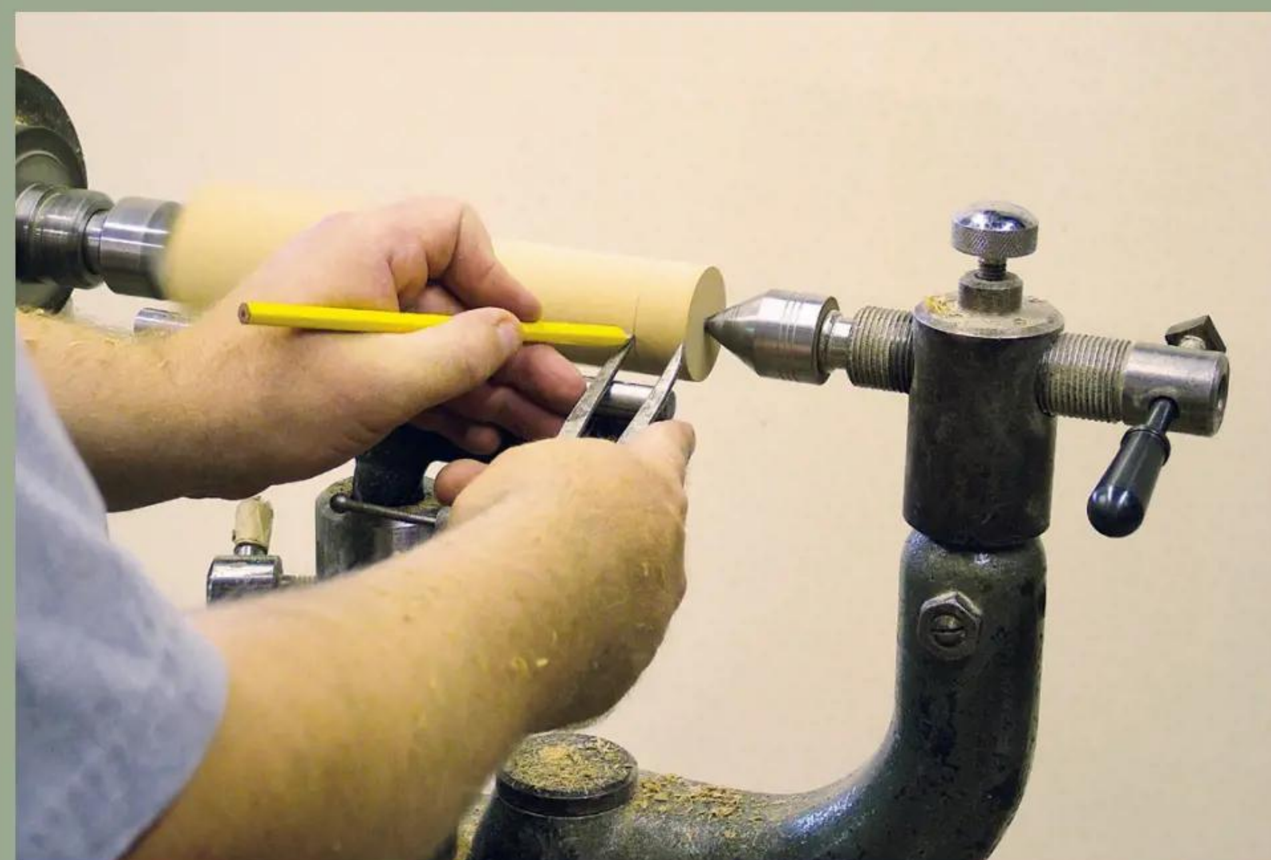
16 Mark a line with callipers and pencil 12mm from the leg's foot
