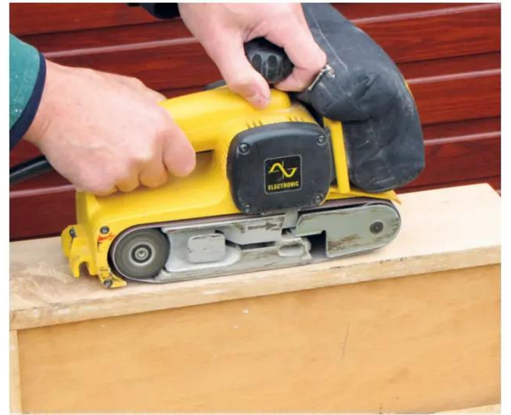
5 Although a belt sander can be pretty aggressive, it's a great tool for cleaning up wide, flat areas...
