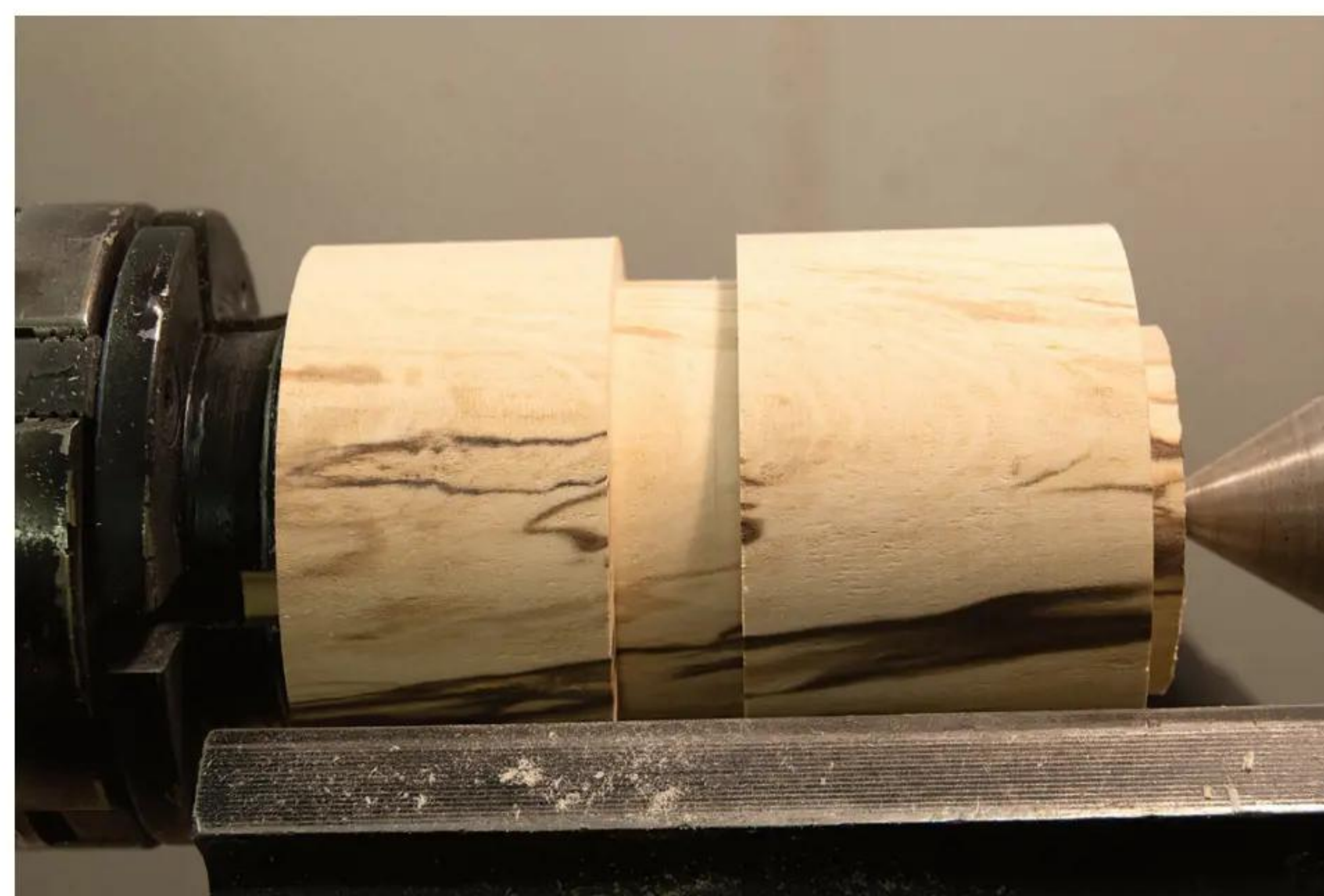
3 ... the diameter of which will determine the lid's wall thickness, as it needs to fit with the base's top
