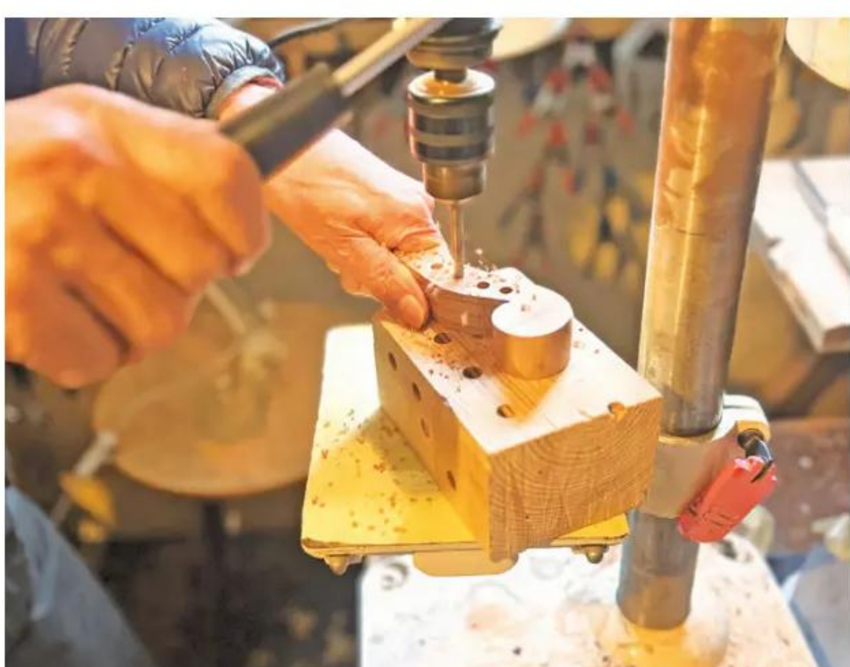
14 Drilling the peg holes
