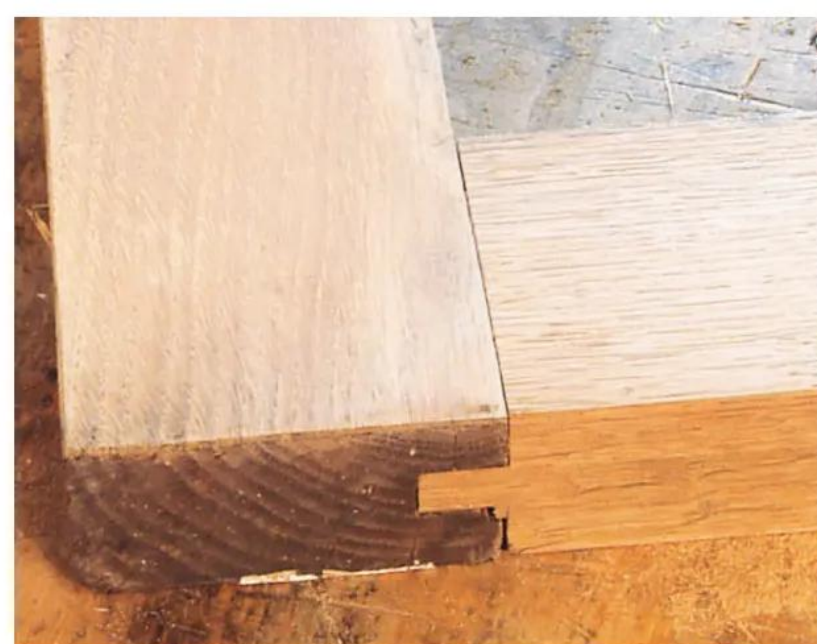
14 The rail and stile once assembled
