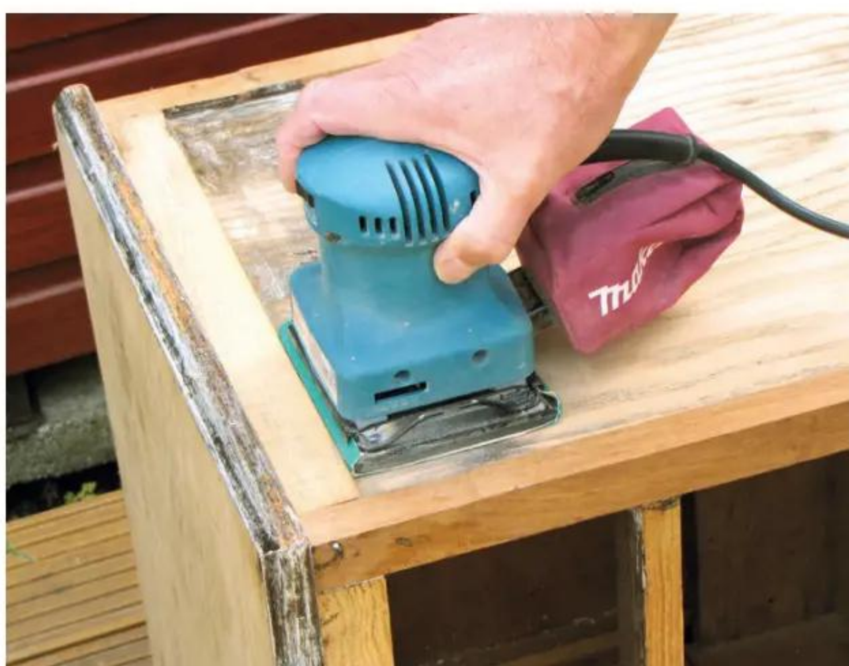
6 ... while a palm or detail sander is ideal for getting tight into corners; however, hand sanding will still be required
