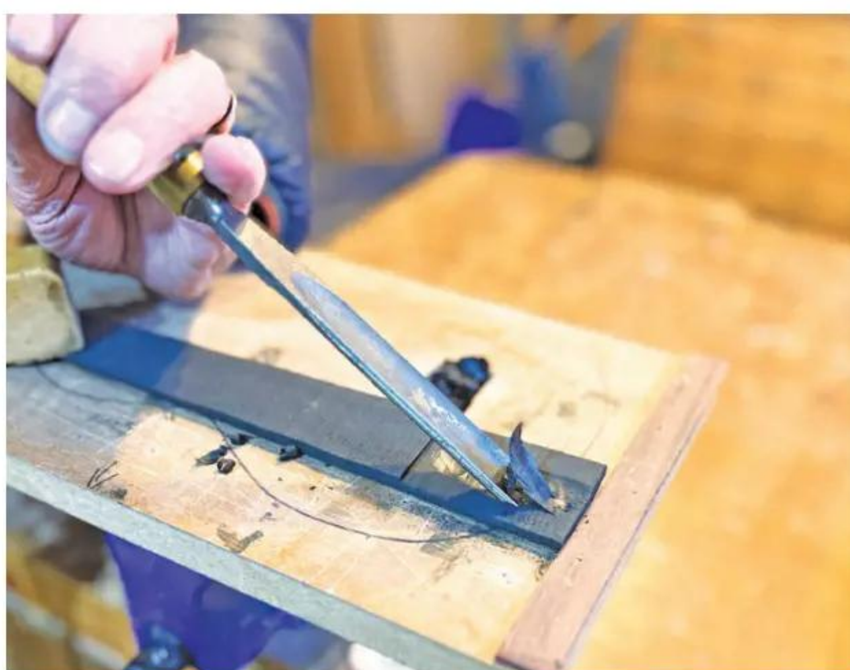
21 Fingerboard's lower inside section once hollowed
