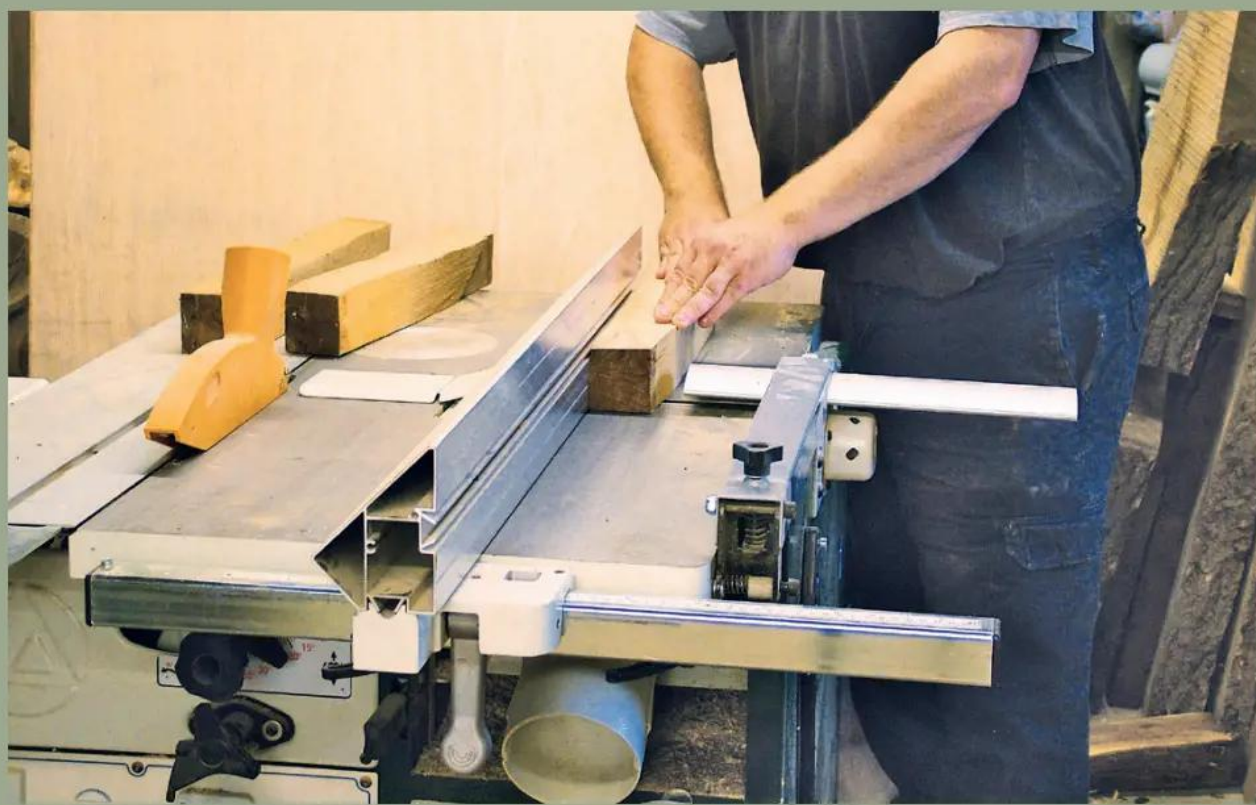
3 Pass two adjacent edges over the planer to create a square corner
