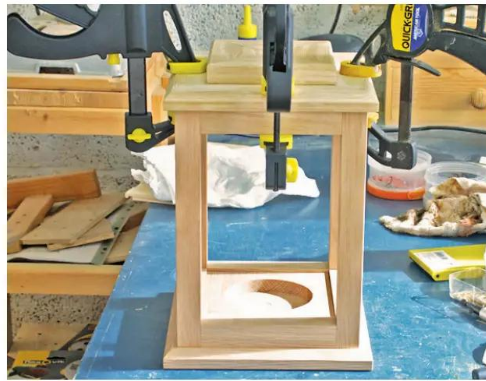
18 I attached the top assembly using exactly the same method, then inserted and glued a piece to keep the vase and candle in place
