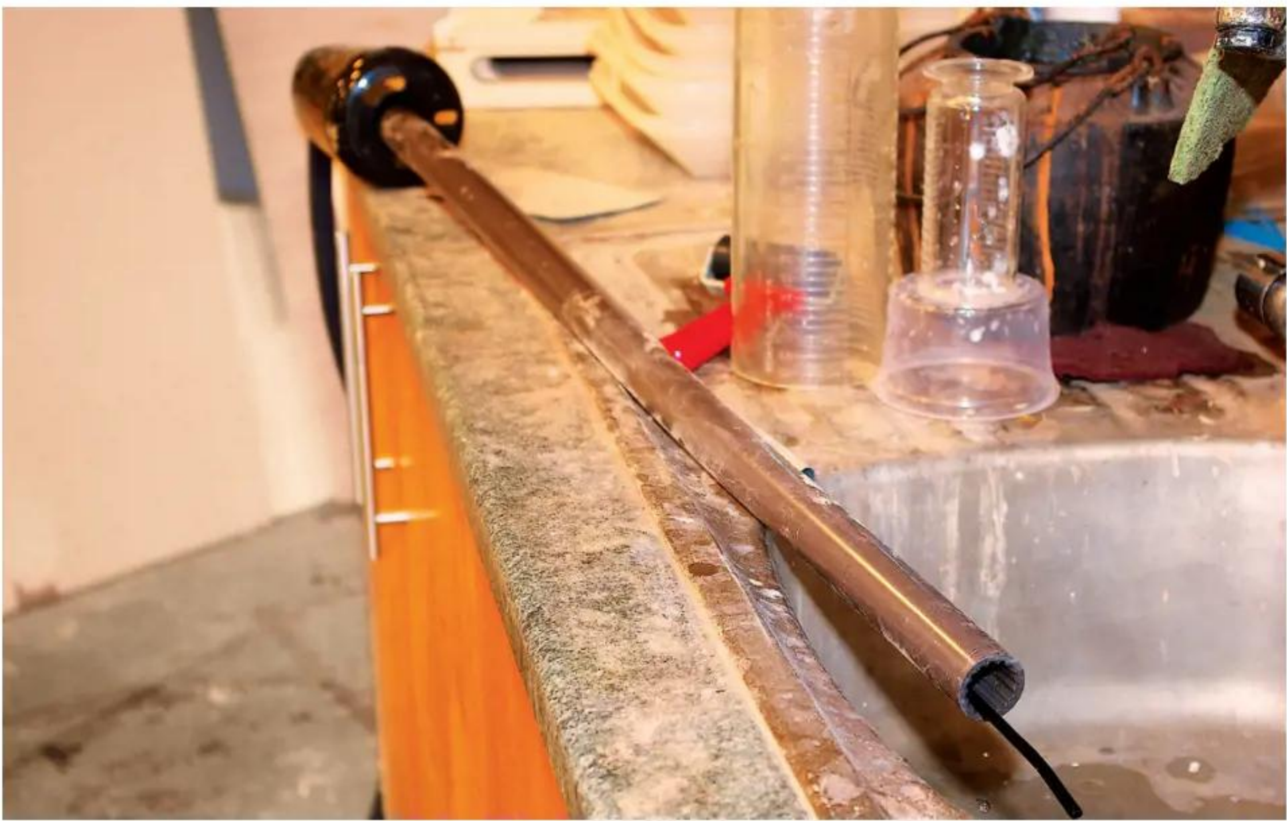
19 A wallpaper stripper and piece of pipe are just the job for steaming the brittle ebony seen here
