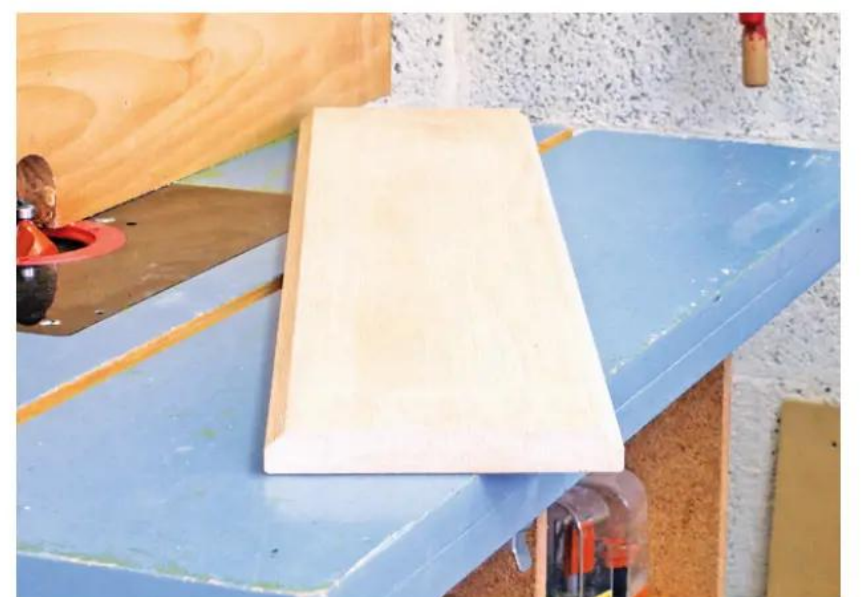
12 To produce a true 45°, I made my timber the correct thickness but a little wider than required, then cut the chamfer equally on both sides
