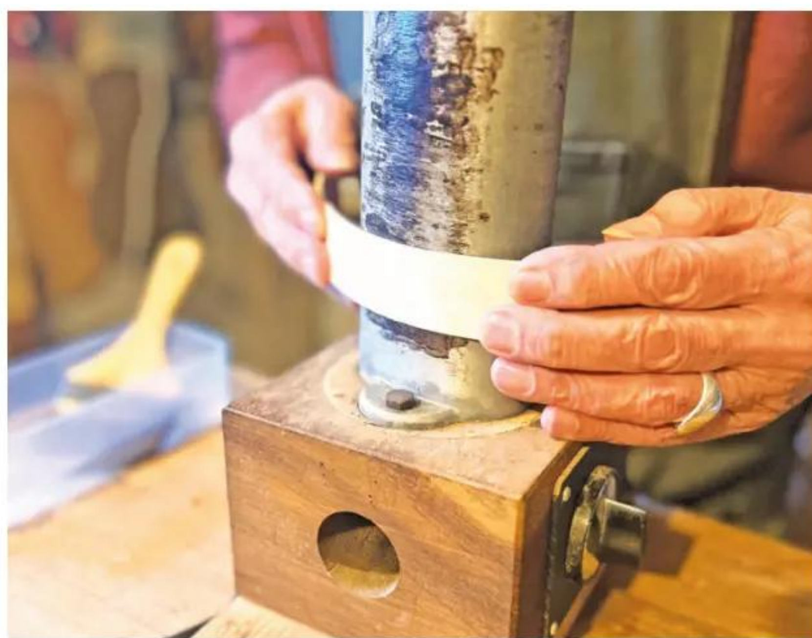
8 Bending the sides on a heated iron
