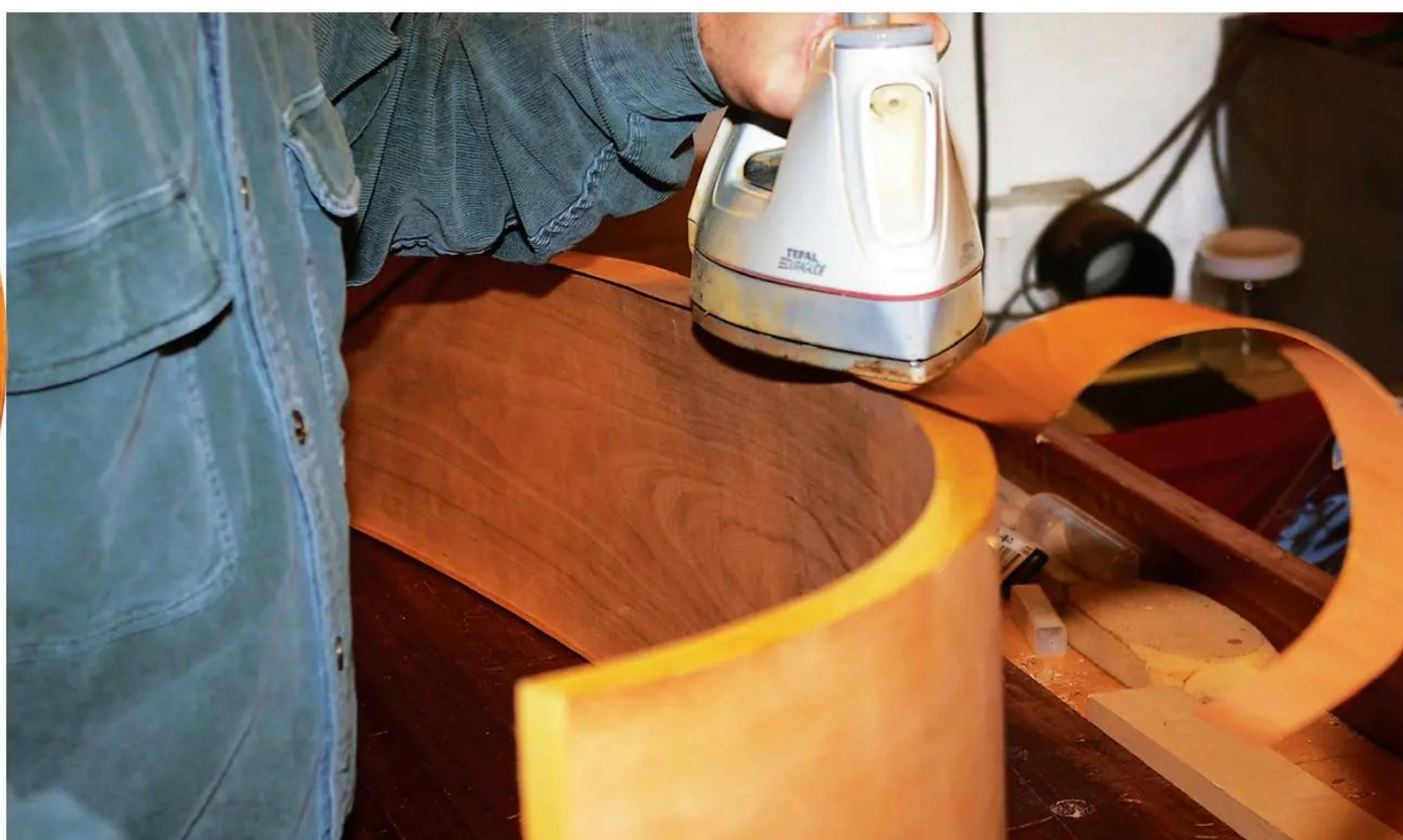
17 Iron the veneer into place, ensuring it's completely attached
