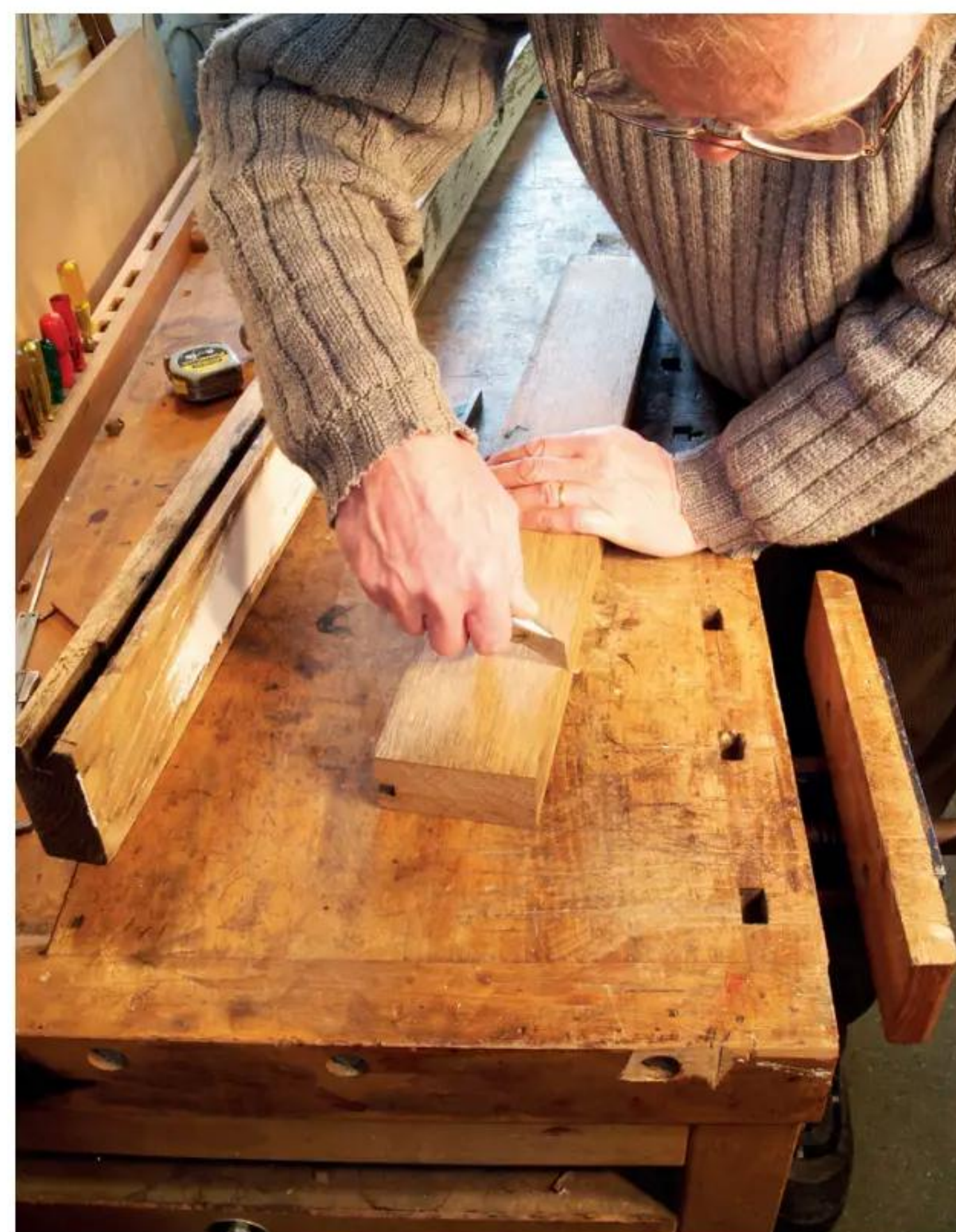
7 A little knife line that goes across the arris helps square around
