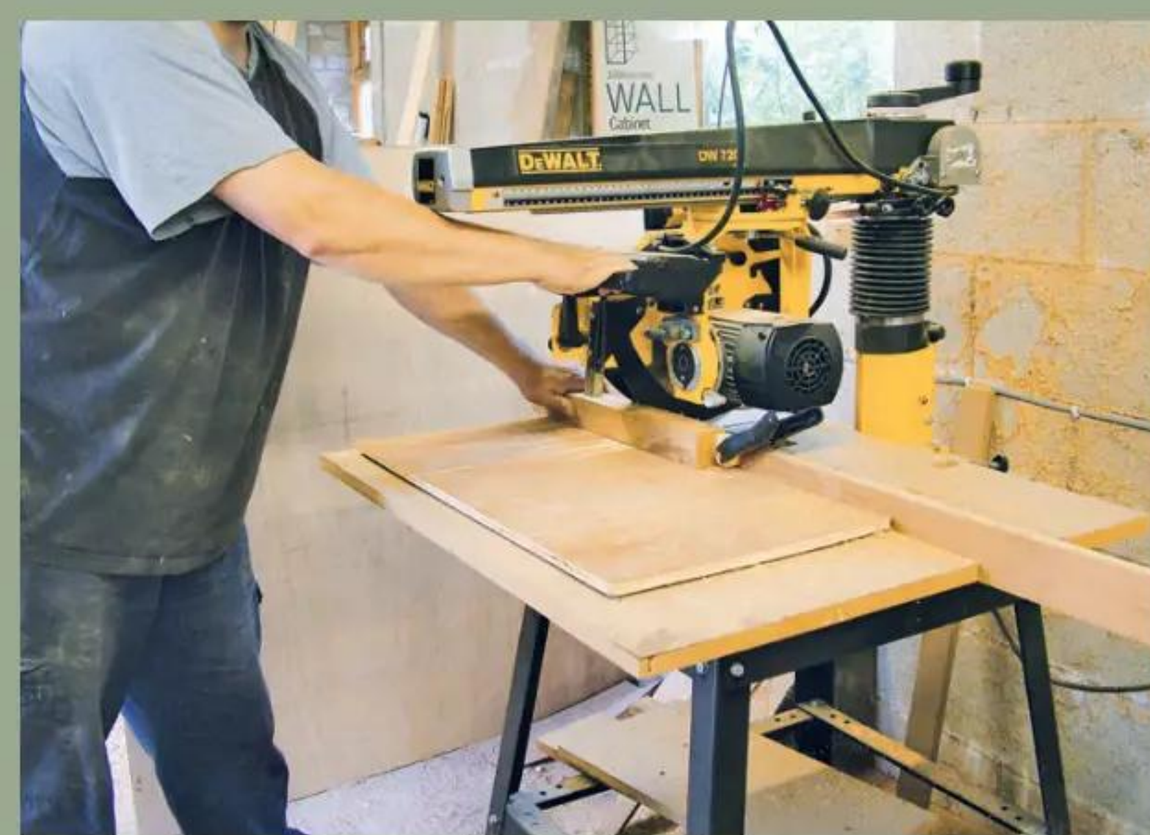
5 Cross-cut the blanks to length. Here I'm using my radial arm saw for the job
