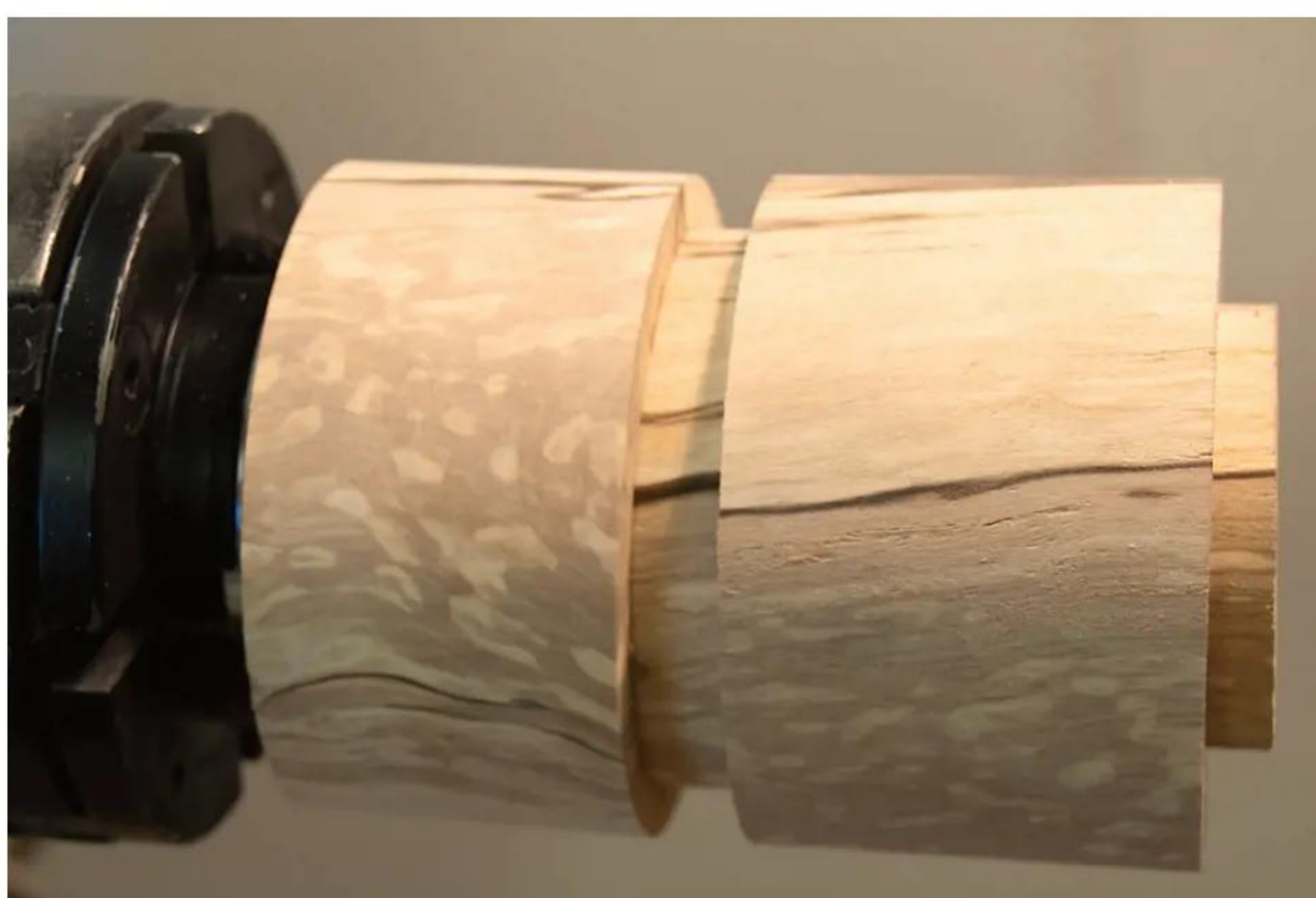
7 I made it too loose on purpose – honest! The lid needs to be a really tight fit, so ensure to remove small amounts at a time
