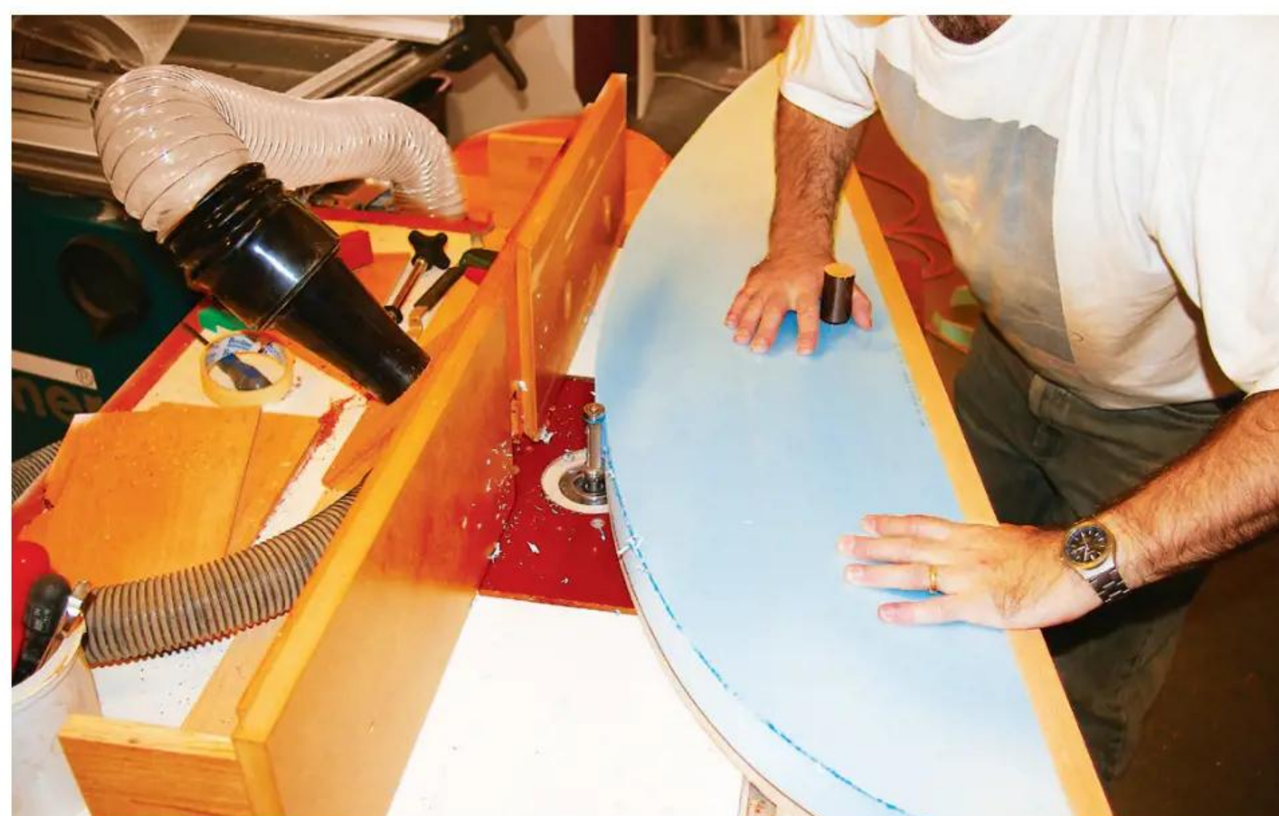
4 ... and finish on the router table using a bottom bearing-guided cutter
