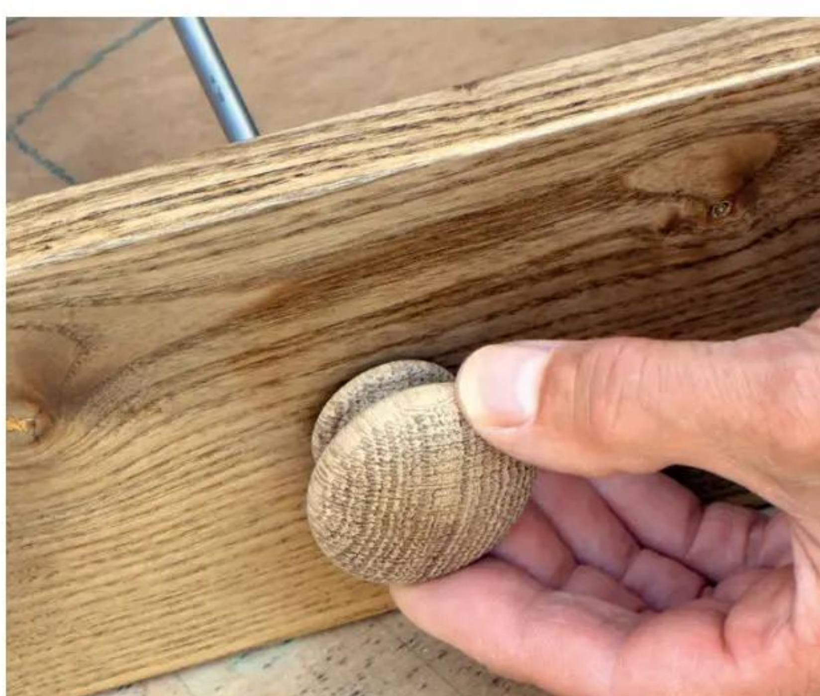
13 If some drawers are lighter than others, darken with coloured wax; screw new knobs to the fronts to complete
