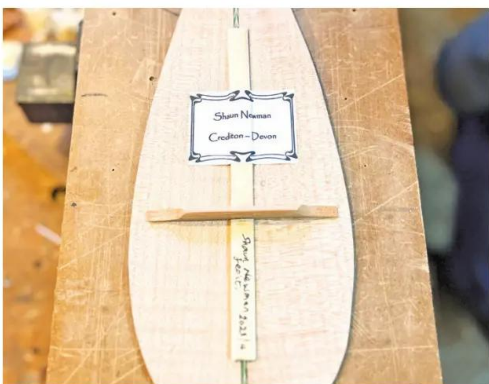
11 The back is braced and maker's label fitted
