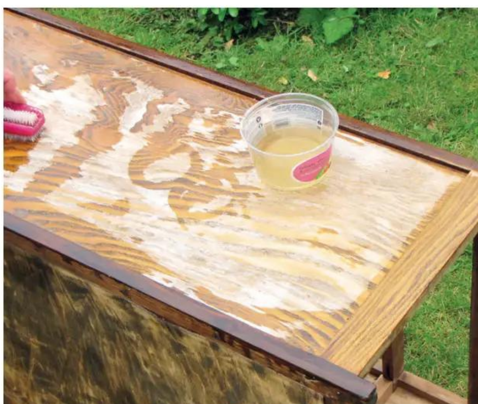
10 The bleach now needs to be neutralised with water; if stains persist, repeat the bleaching process
