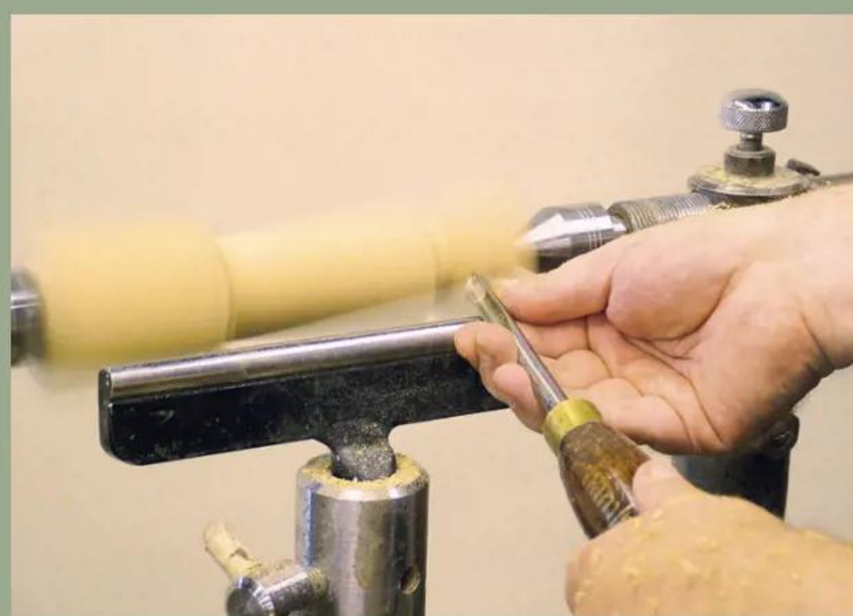
18 Cut a cove in the leg's offset part, to the left of the pencil line
