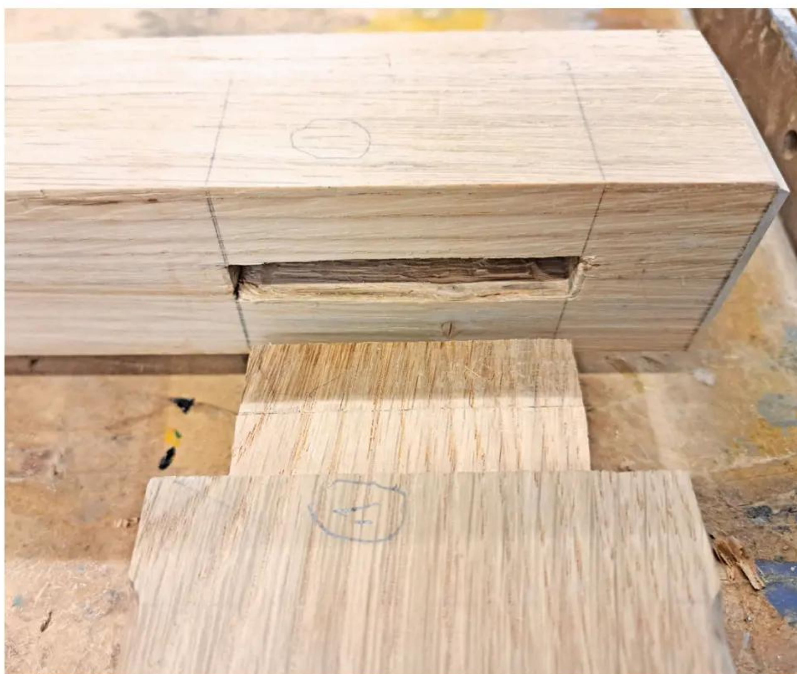
1 One of the mortise & tenon joints, for the point at which the front rail meets the legs
