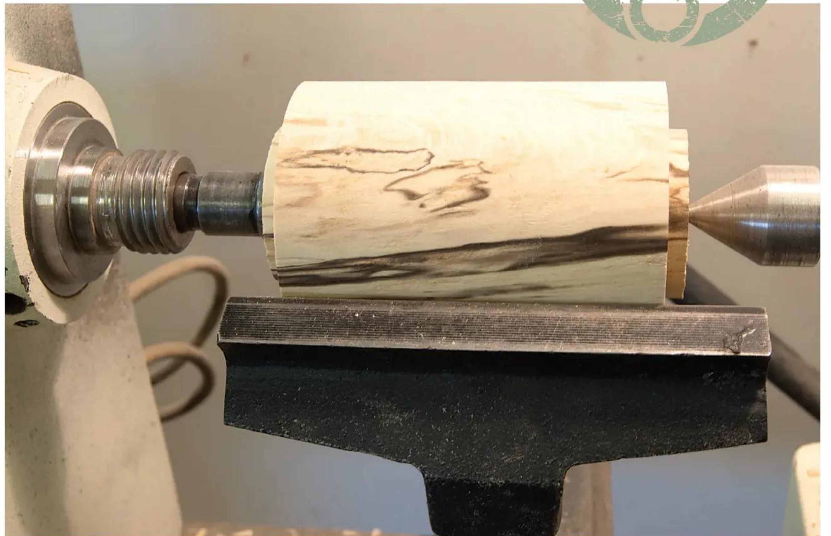
1 Mount the timber between centres and turn round using a spindle roughing gouge, forming spigots on both ends
