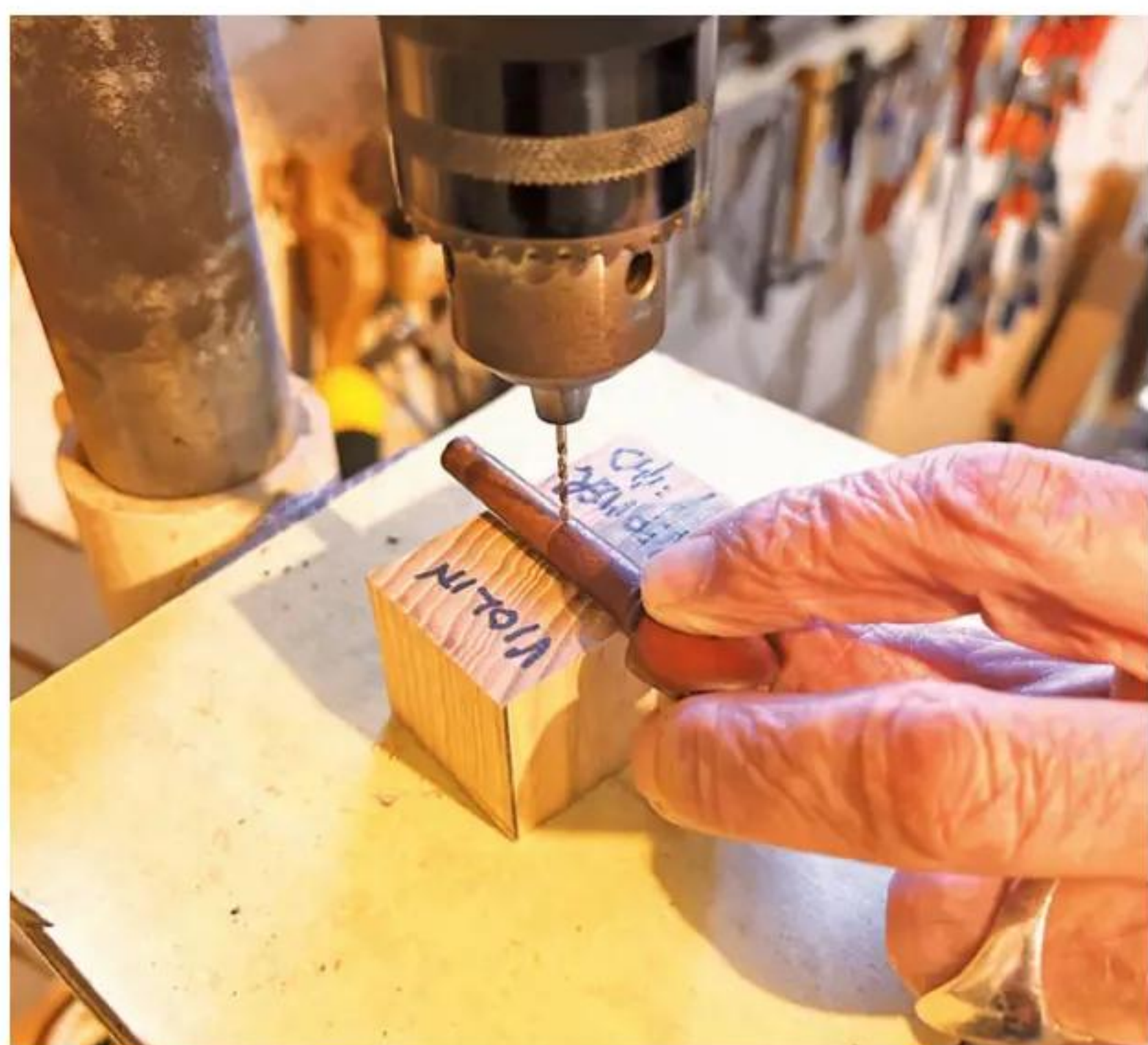
26 String holes are drilled into the pegs
