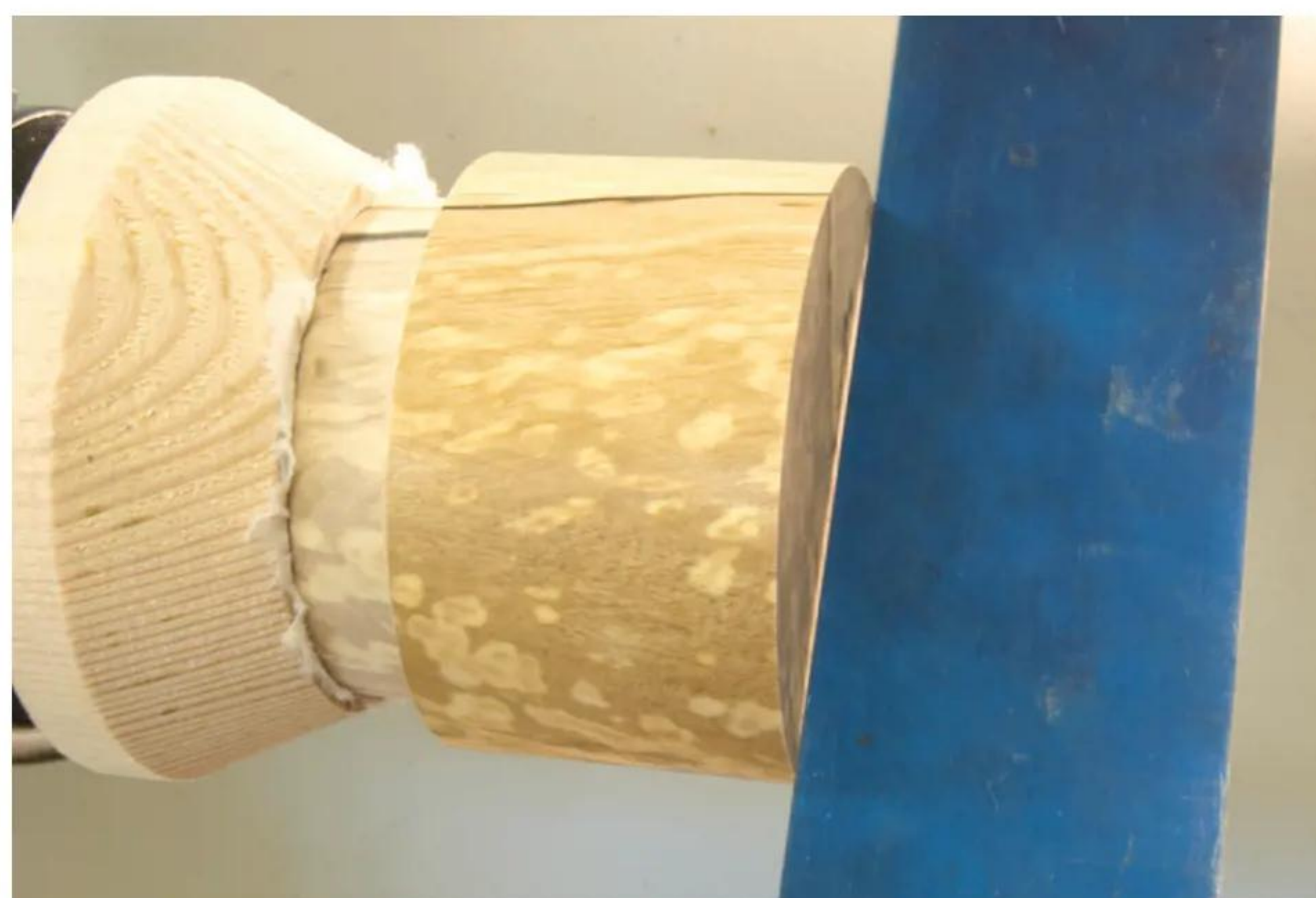
17 ... and put a slight concave shape into the box's base, so that it always sits on the outside edge
