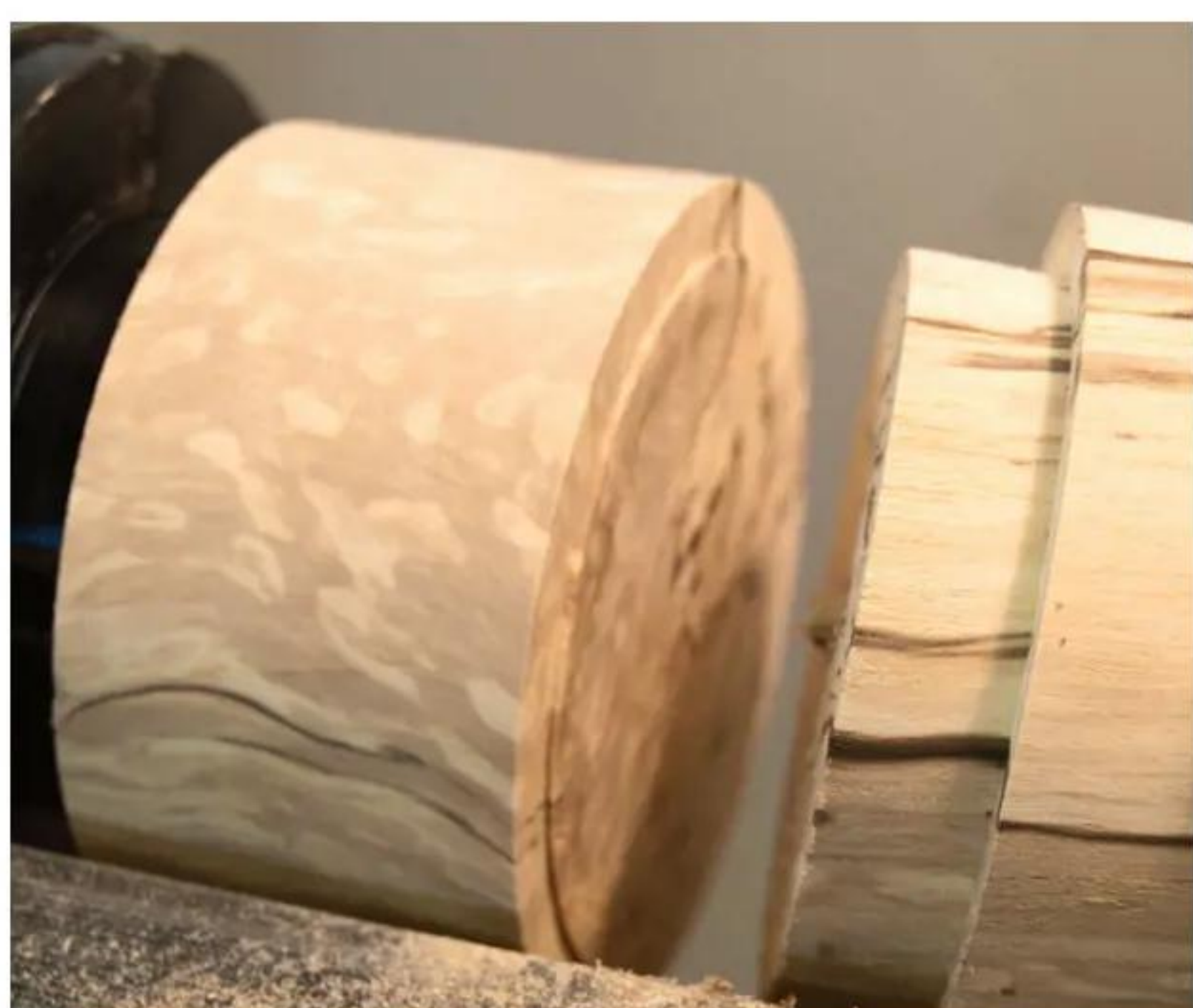
4 Note the tiny ridge that denotes the spigot's diameter
