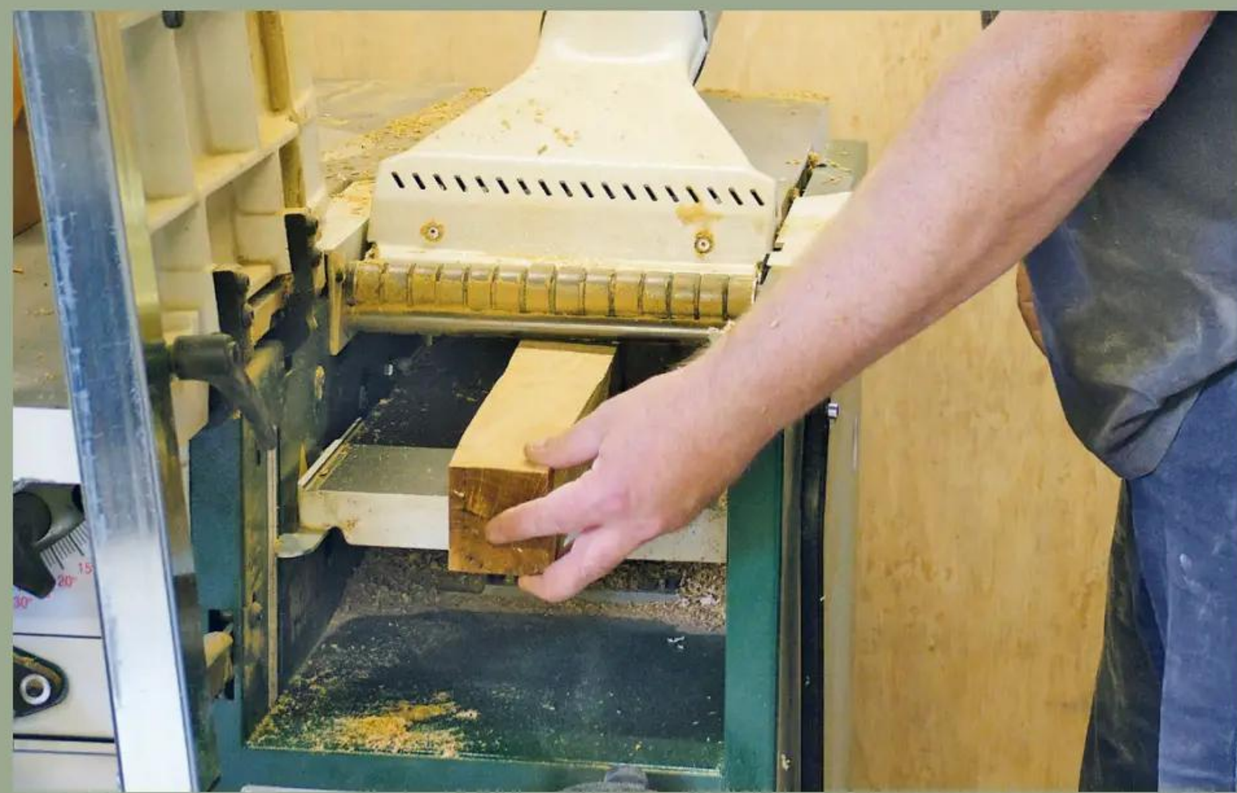
4 Plane the other two faces on the thicknesser to make perfectly square stock
