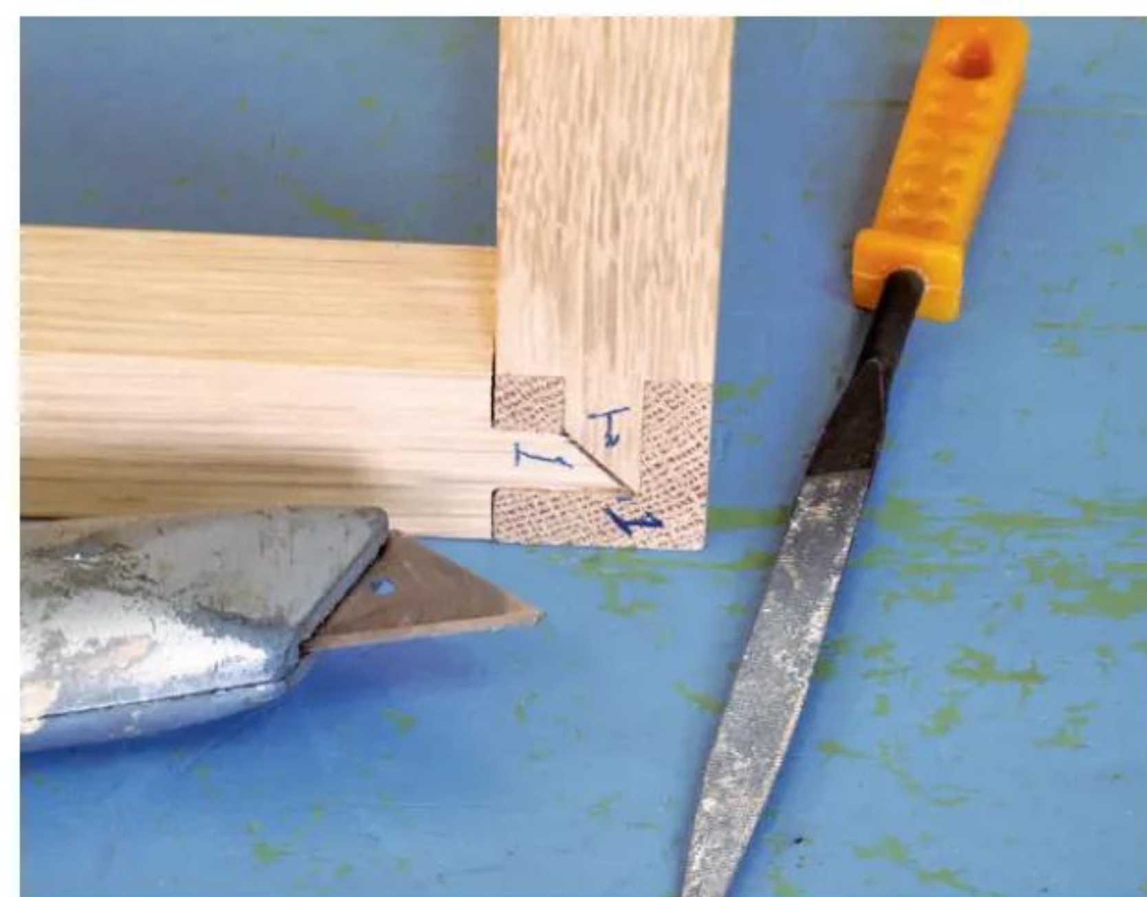
6 I used a craft knife to remove the bulk of the material, then employed a small metal file for final shaping, before checking to ensure all tenons were properly seated
