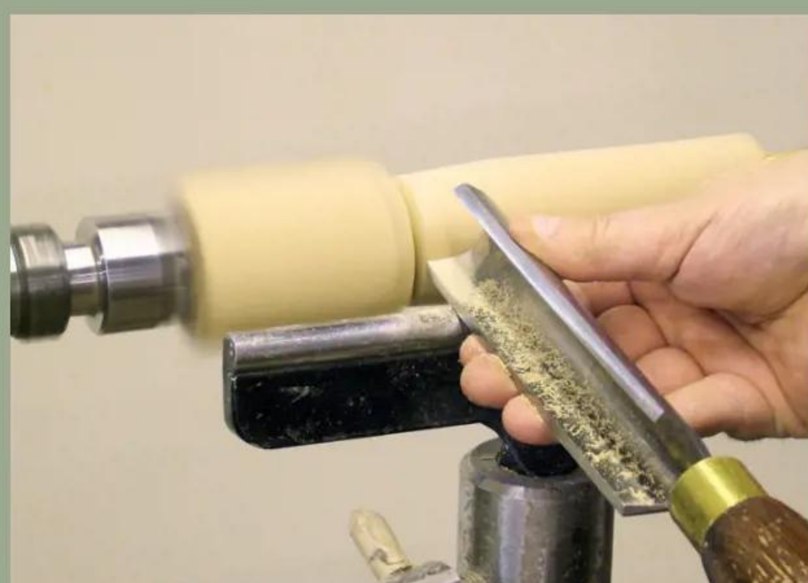
14 Use the gouge on its side to avoid contact with the square section
