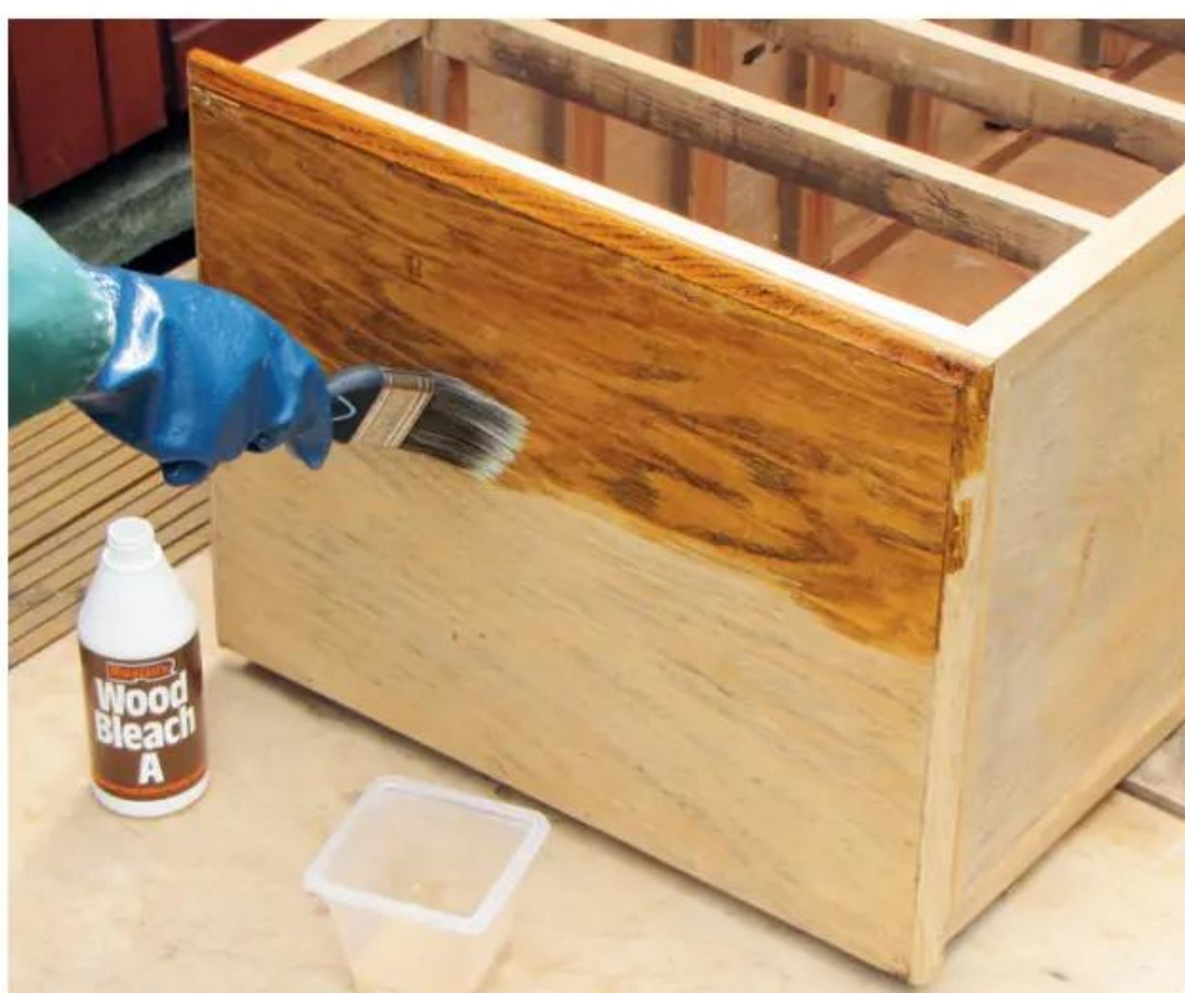
9 When sanded, brush on the activating solution and allow to dry, then apply the bleach in the same way
