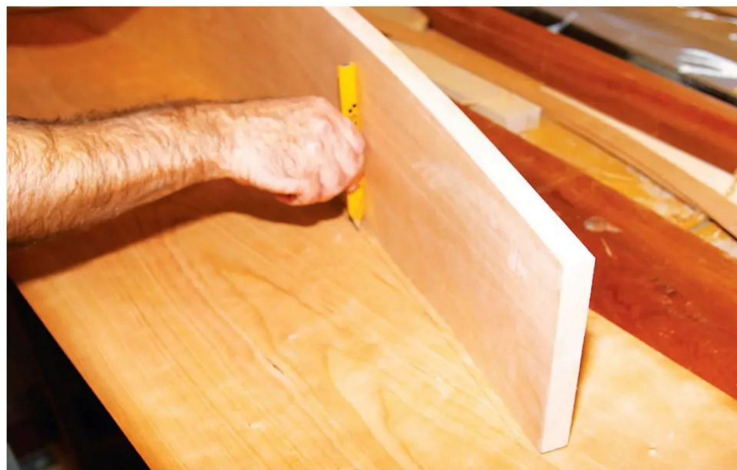
14 After trimming the veneered faces with a block plane, mark out cherry veneer for the edges
