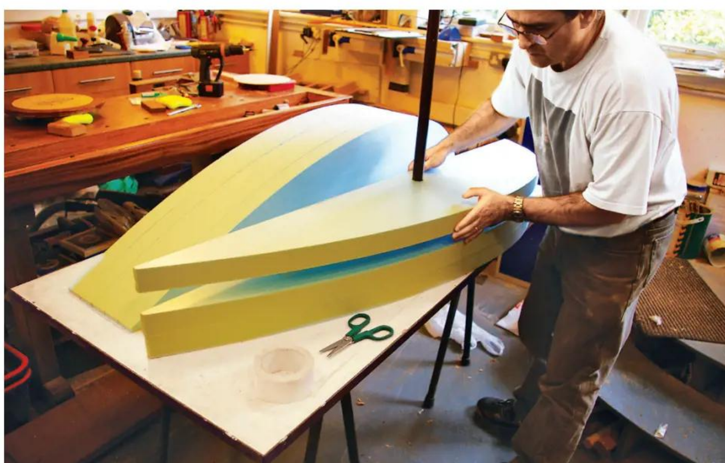
5 Fit the separate blanks over the dowel and join them with double-sided tape
