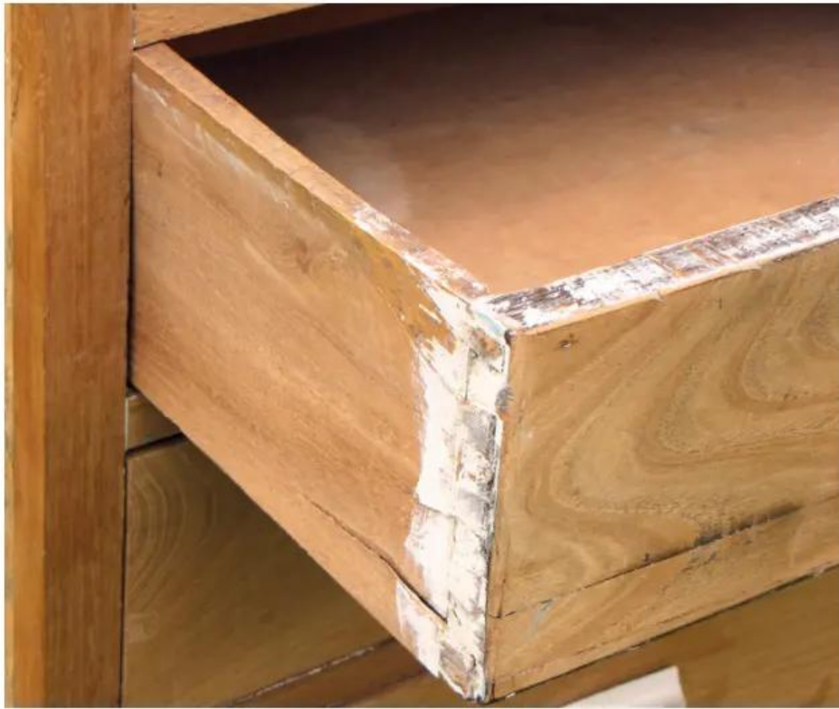
3 Some drawers may be worse than others; although these fronts are dovetailed, backs are only nailed to the sides
