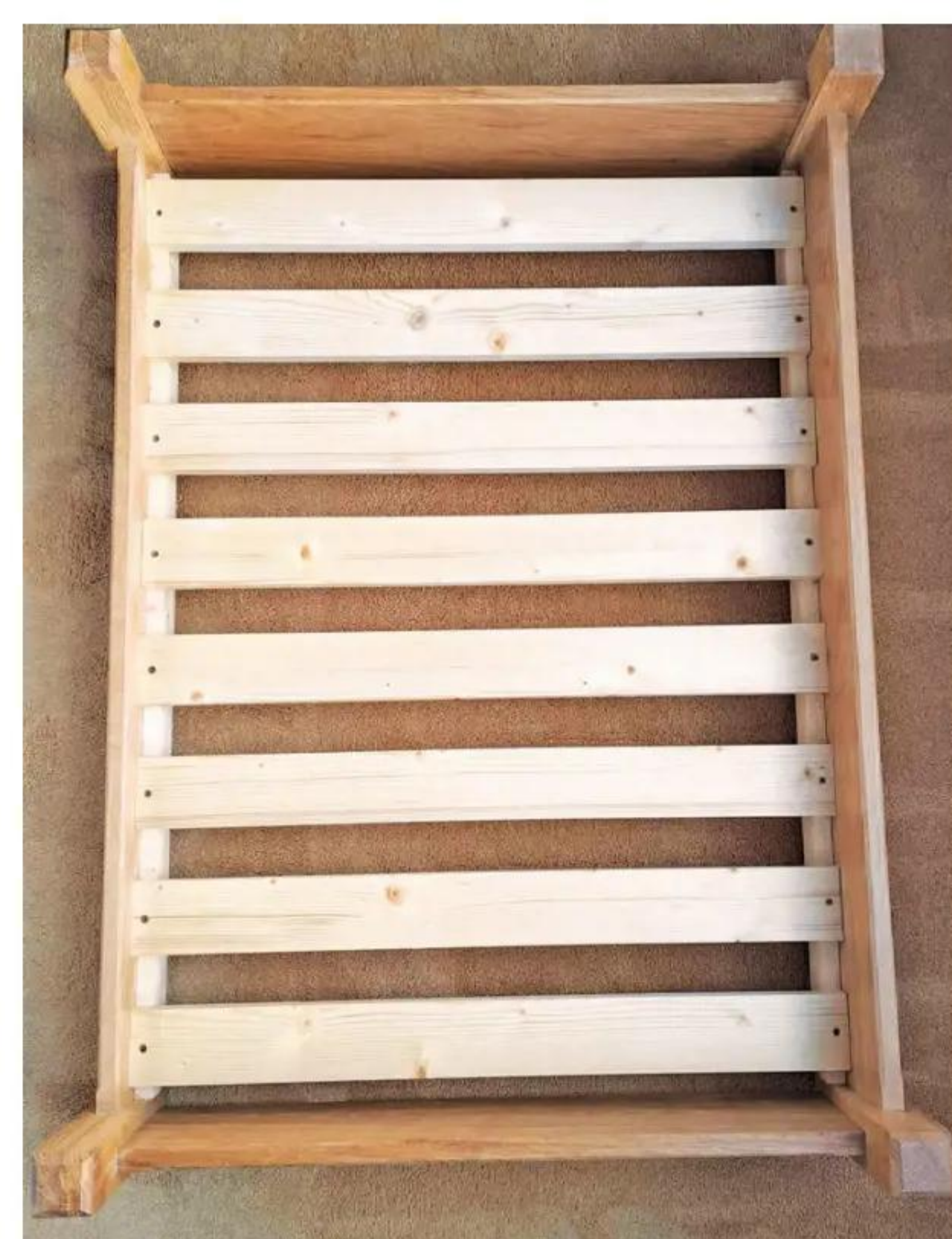
5 The 75 x 25mm pine slats were screwed in place, but not glued
