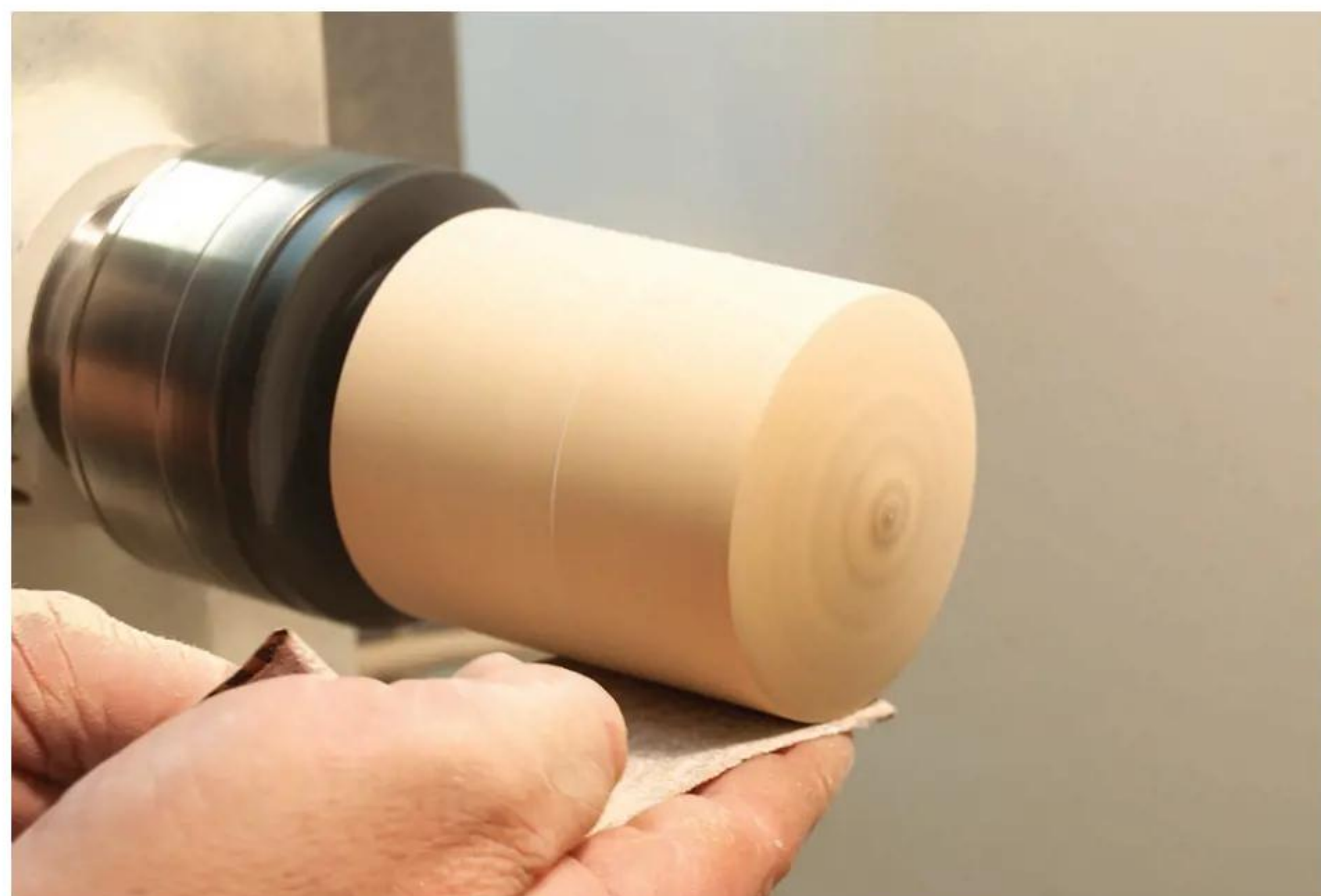
10 Sanding – my favourite pastime – not! Use abrasive and work through the grits to remove tool marks
