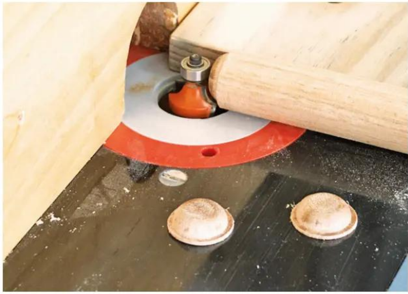
19 Using any shop-bought wooden handle of a suitable size and timber, spin it against the stop and bearing to machine the end
