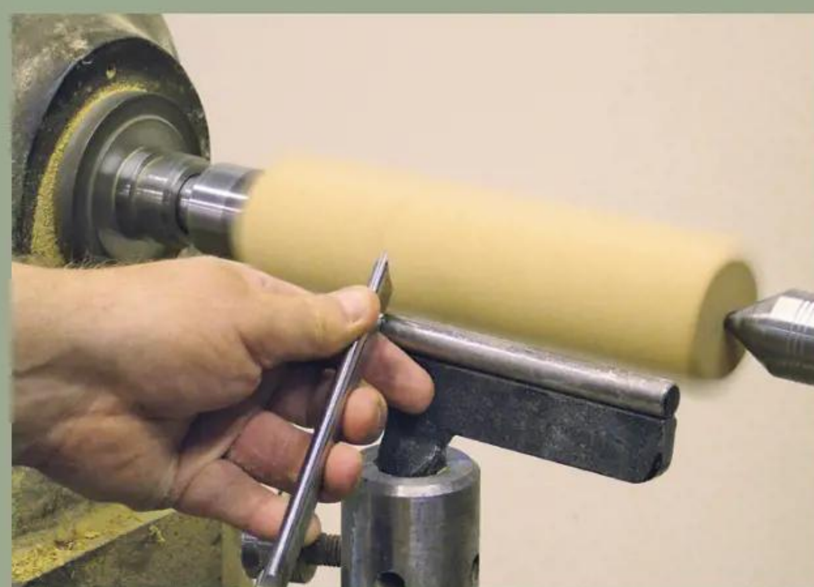
10 Reverse the skew chisel and use it to cut the other side of the 'V'
