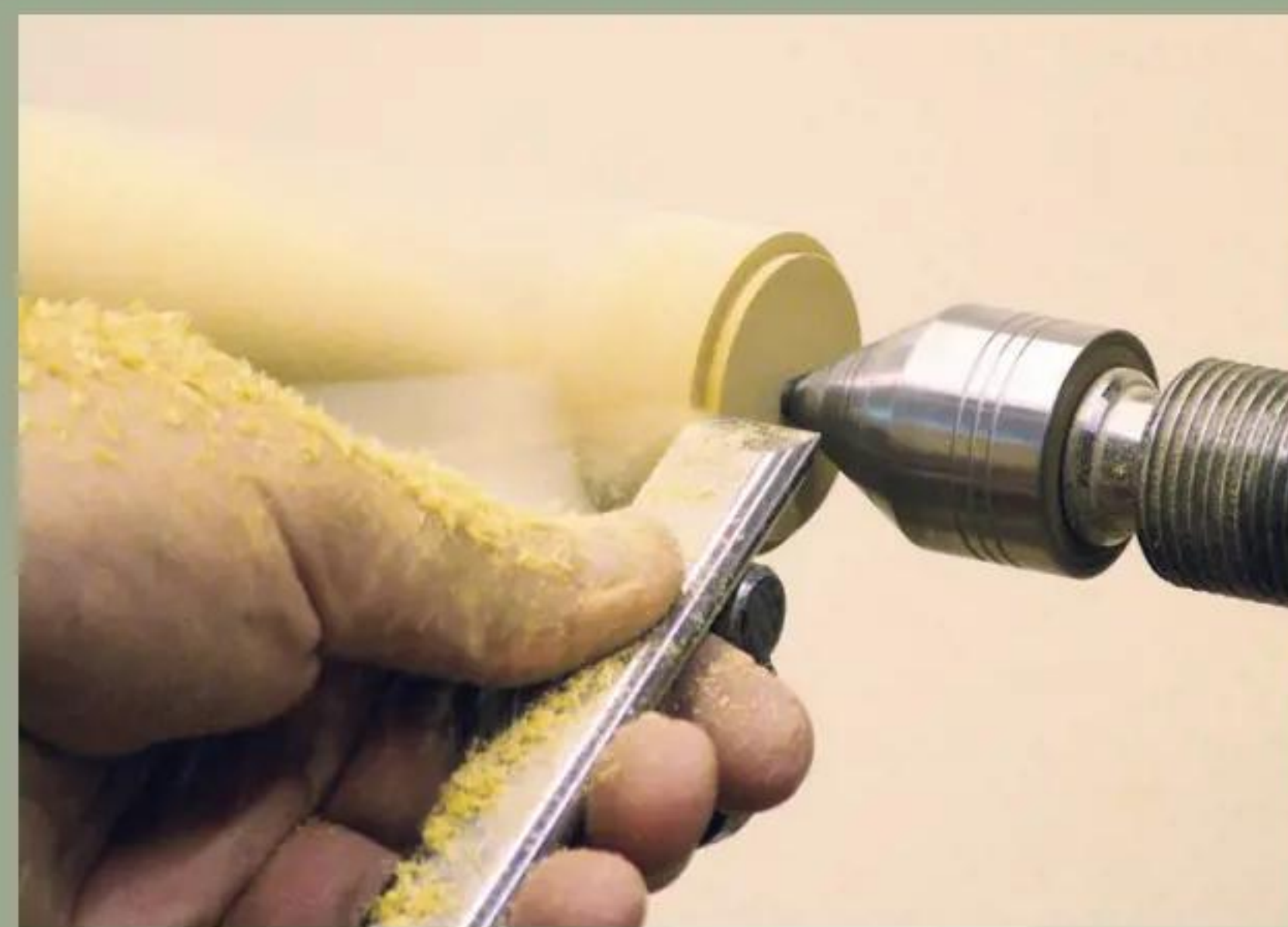
23 Use a skew chisel to make a 3mm peeling cut at the leg's foot
