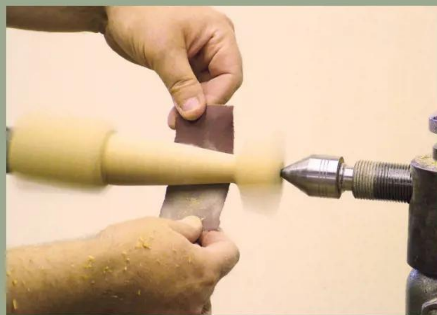
22 Sand this offset part of the leg and put it back on its true centres
