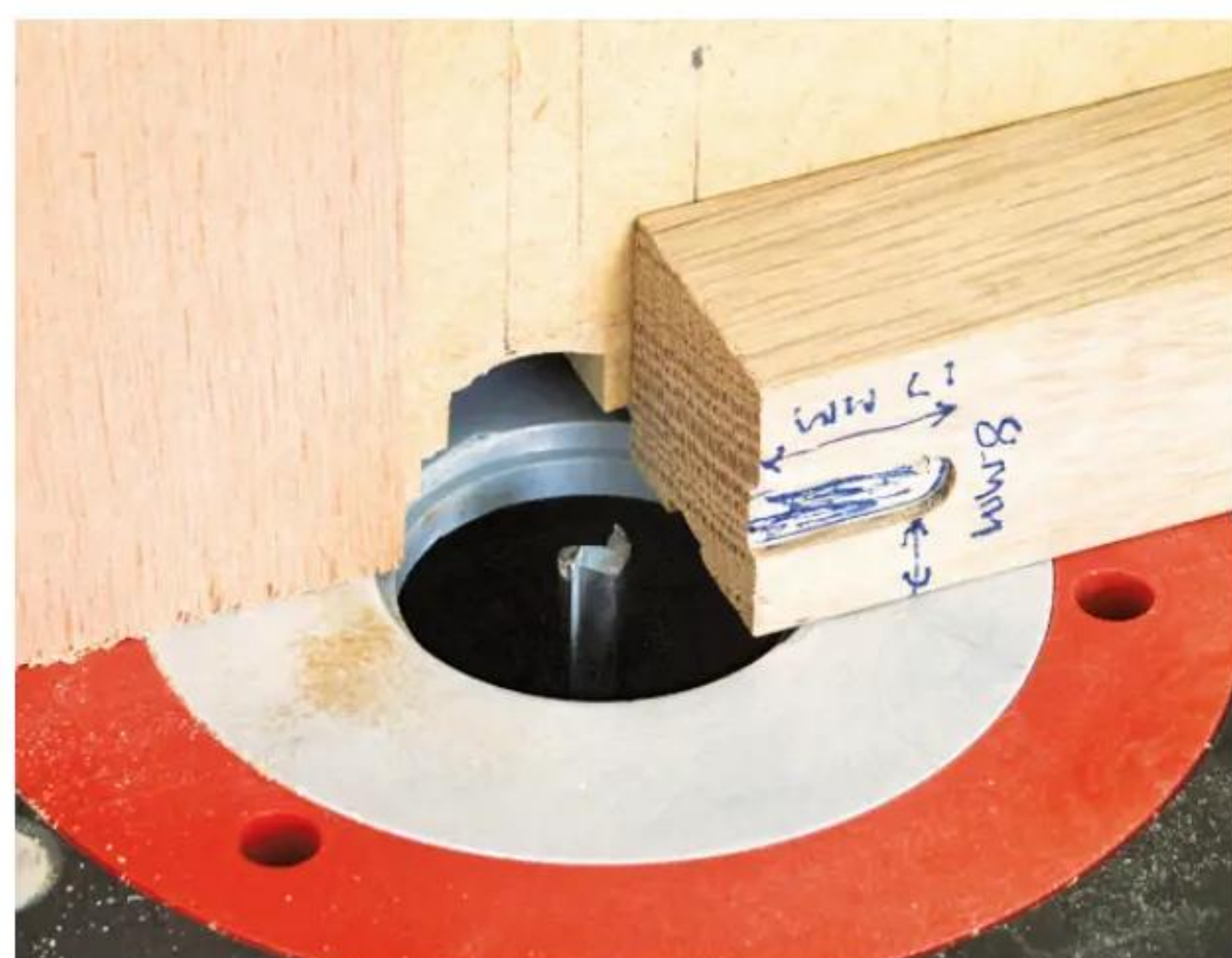
1 Working from the right-hand side of my router table, I clamped a stop to the fence that'd produce a 20mm long cut, using an offcut to set this length accurately
