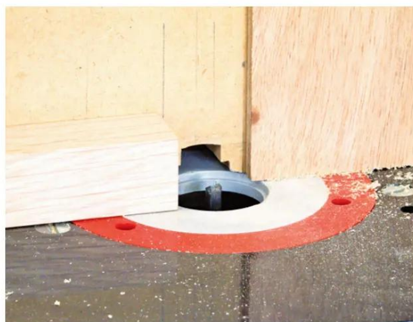
2 I transferred the stop to the fence's opposite side and as before, set the 20mm length using an offcut for accuracy. Working from the other side of the table, I then repeated the process
