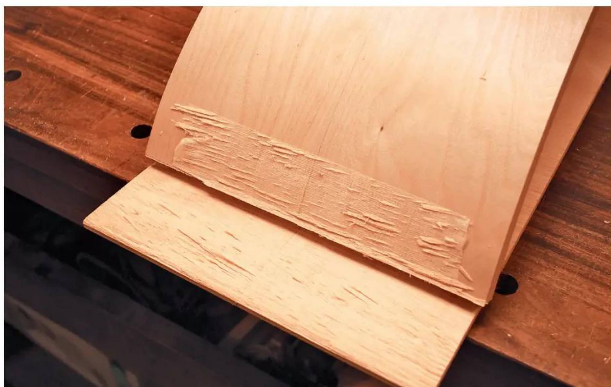
11 Carefully separate the template and leg to avoid damage to the bendy ply face
