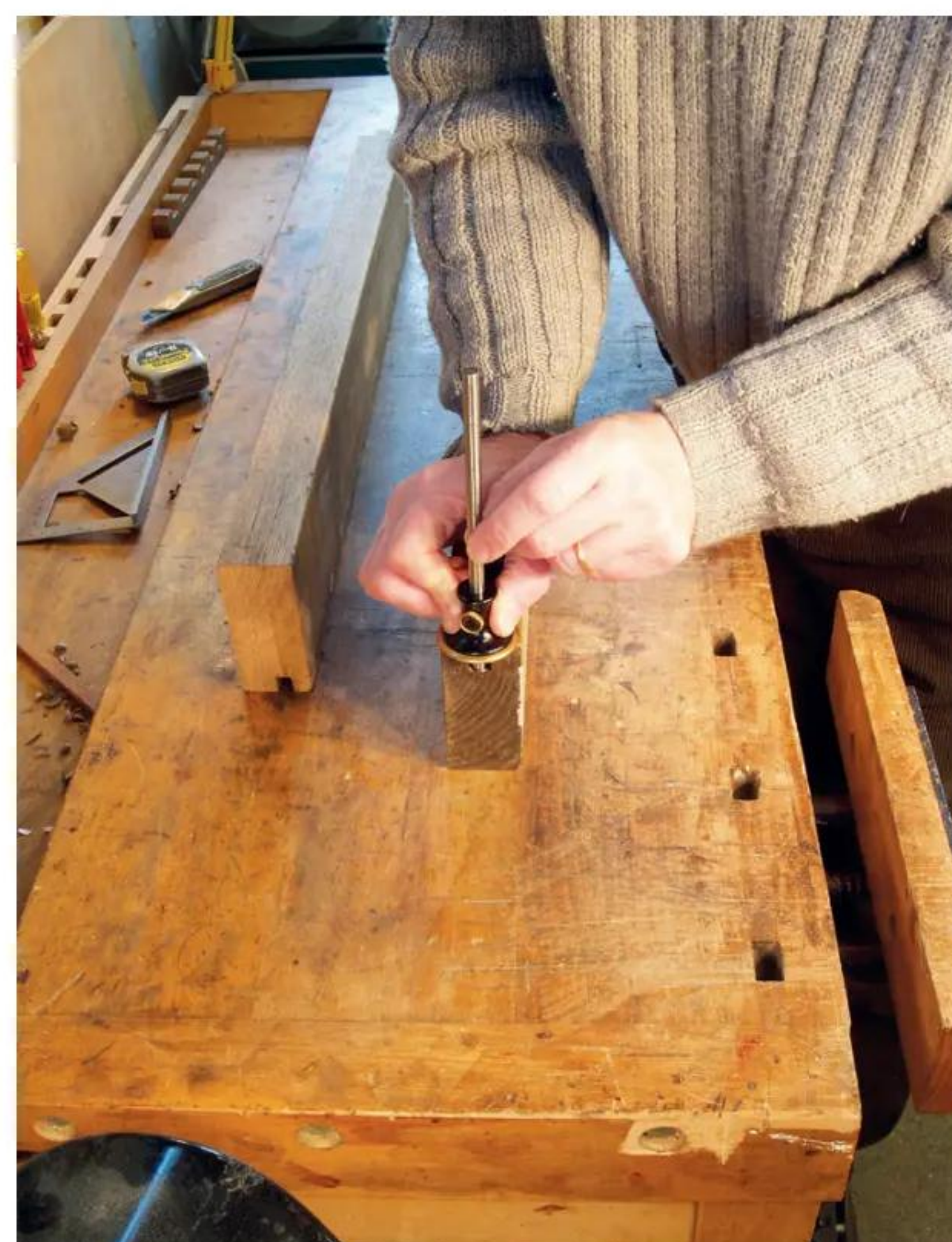
10 Using the wheel gauge as a depth gauge
