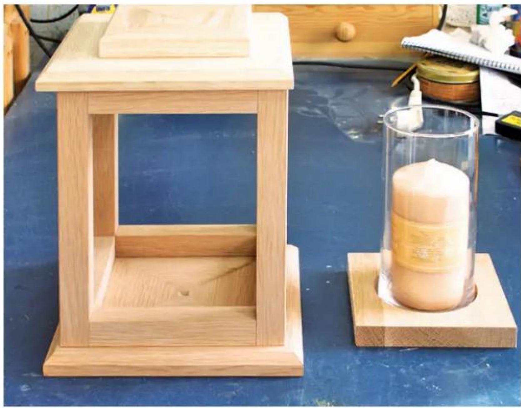
16 I cut an insert to fit snugly into the framework's bottom, then cut a hole fractionally wider than the vase; this helped to keep it firmly in place while still allowing removal
