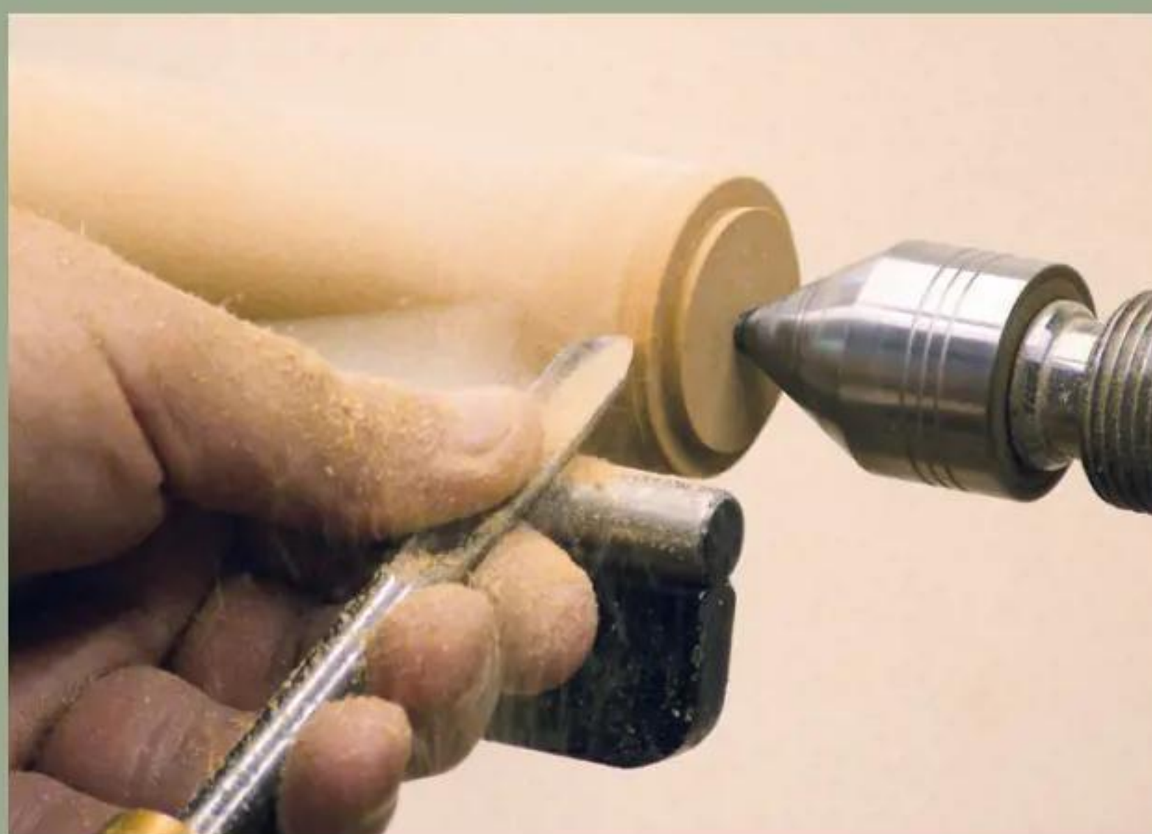
24 Round over the lower part of the foot using a spindle gouge
