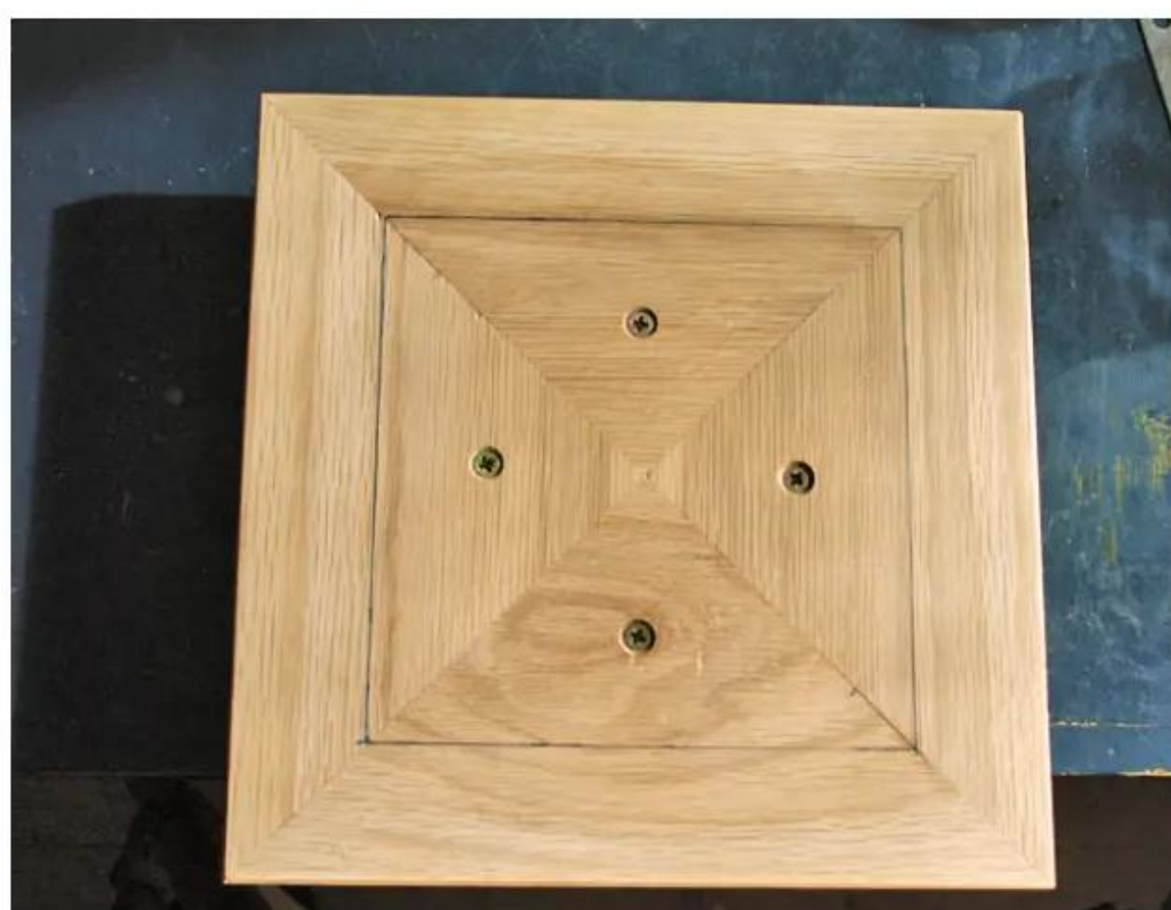
14 Once the glue had set, I inserted the screws
