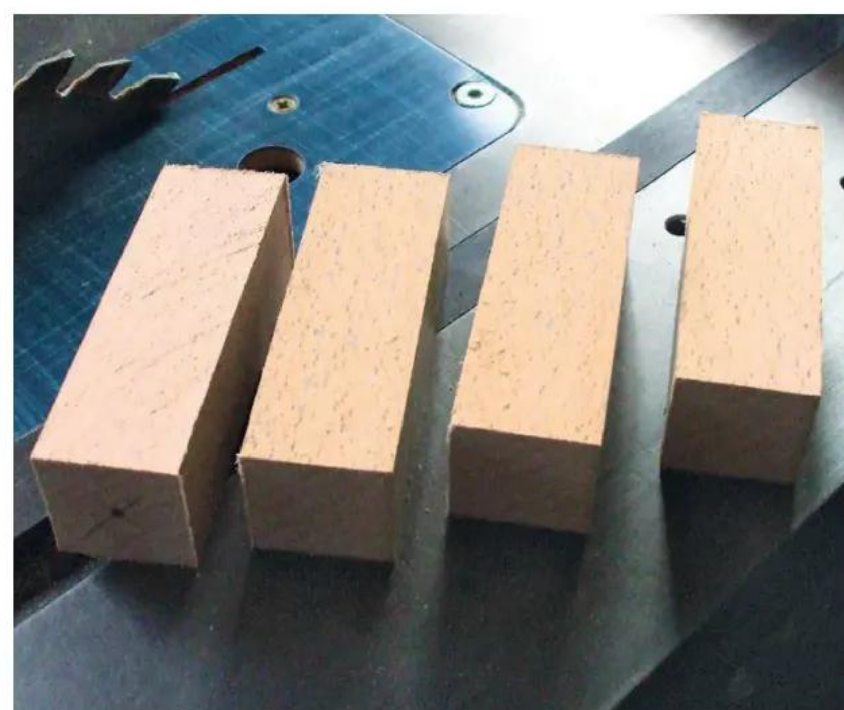
4 Prepare 30mm square blanks about 90mm long for the handles
