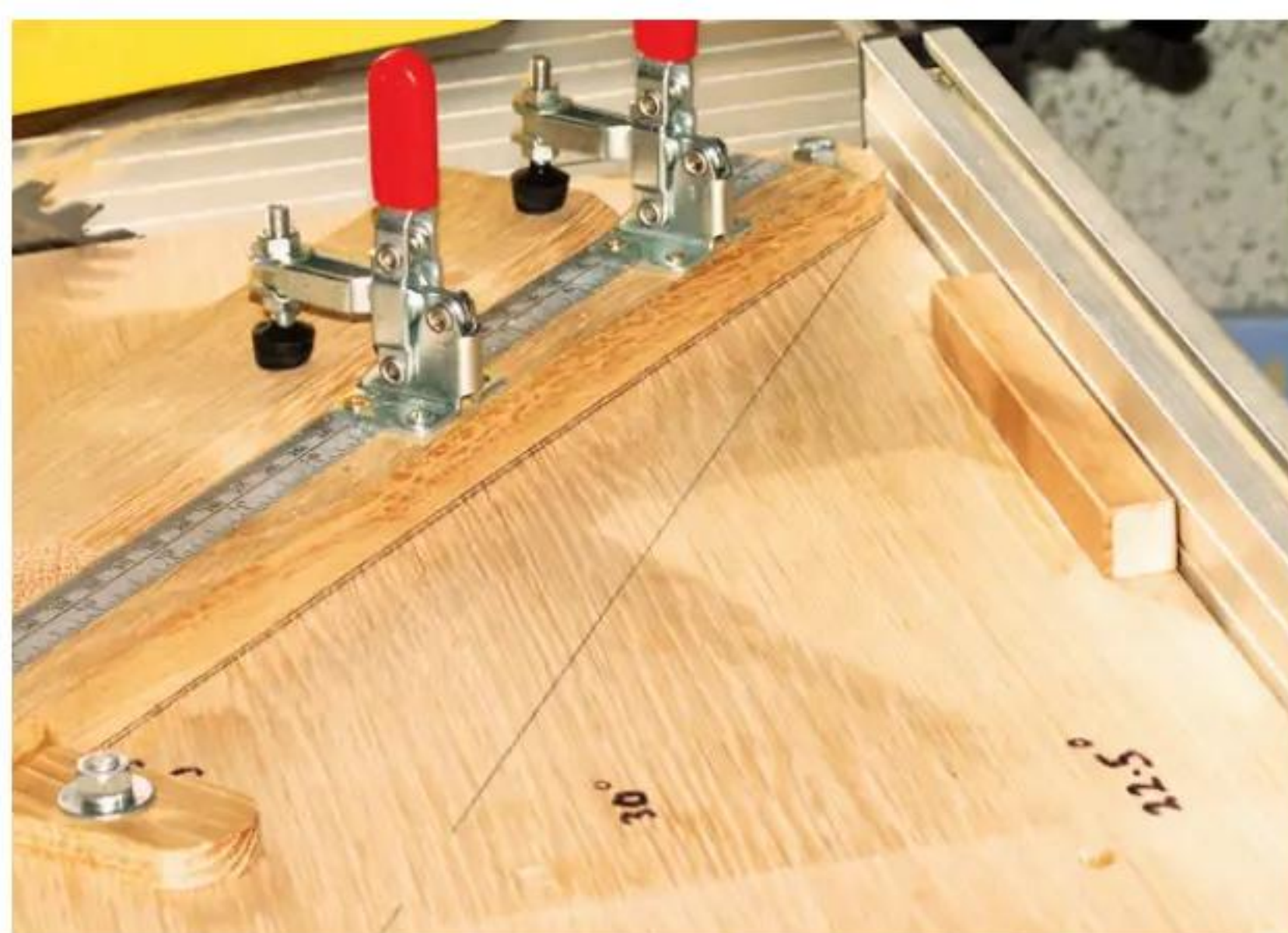
11 I used a dedicated table saw jig for this mitre work, but if your table saw has a sliding table and accurate mitre gauge, this can be used instead
