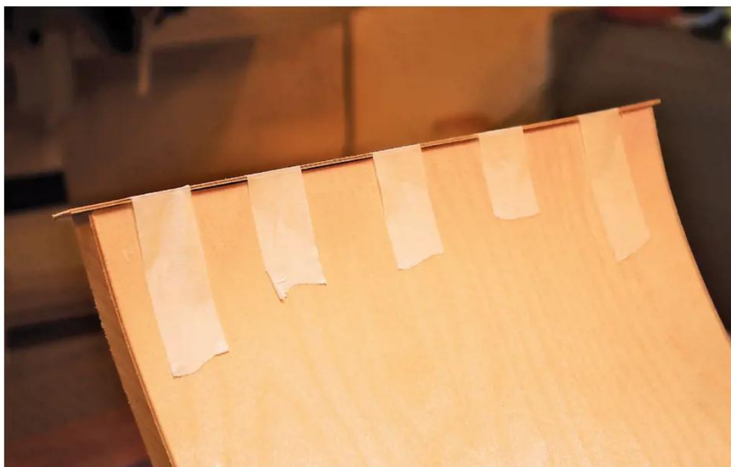
13 Do the same with the leg ends and secure with masking tape until dry
