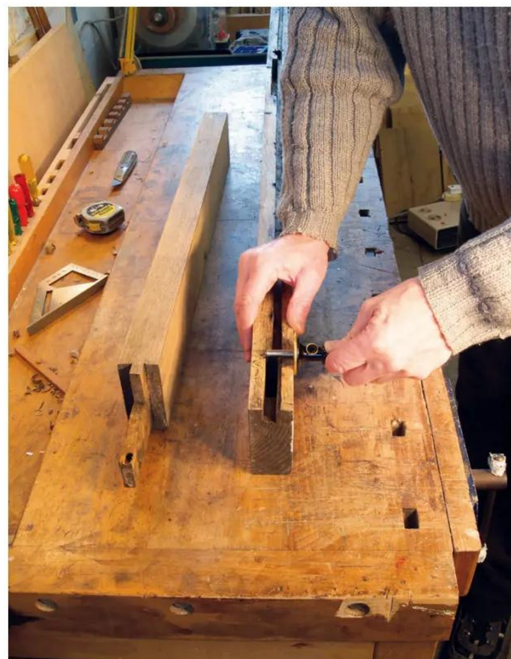
4 A wheel gauge is expensive but easier to set than a pin gauge
