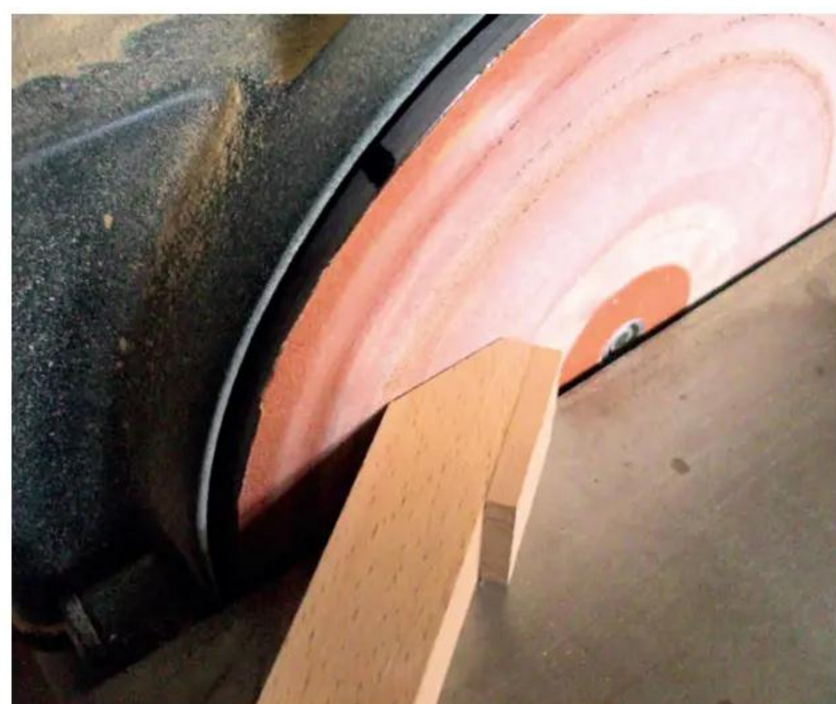
3 Using a disc sander, form a splay on the upper ends of each beam
