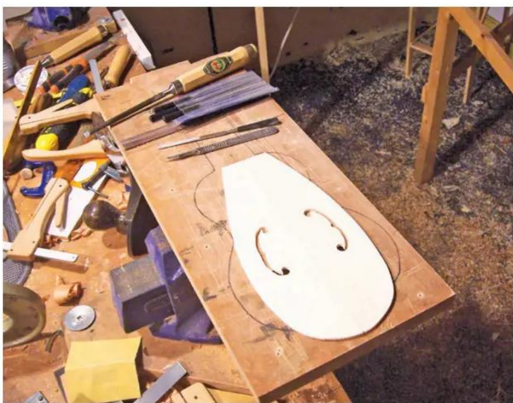
7 Completed sound holes
