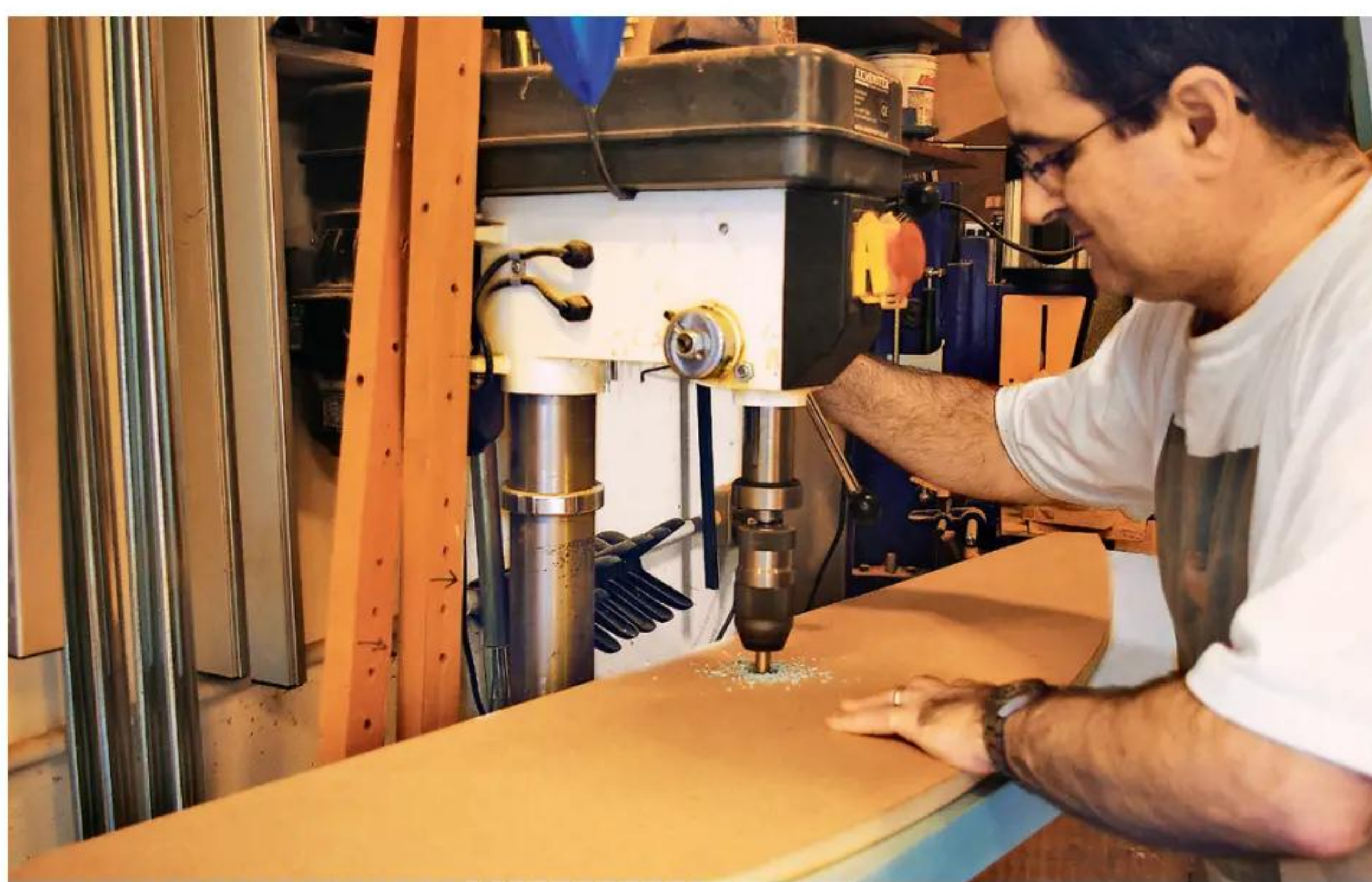
1 While drilling the Styrofoam blanks for the dowel that keeps them aligned...
