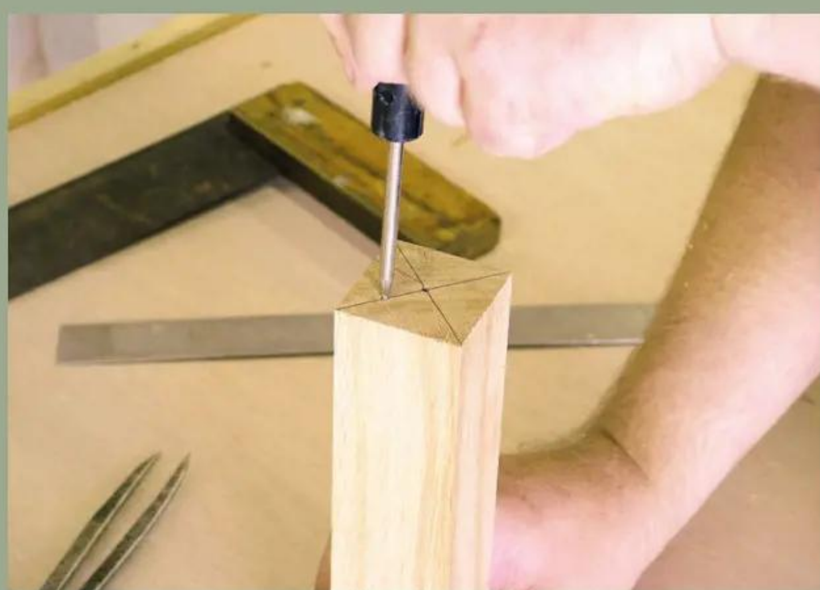
8 Mark a second centre 12mm along one diagonal on each end of the stock; see the text for details
