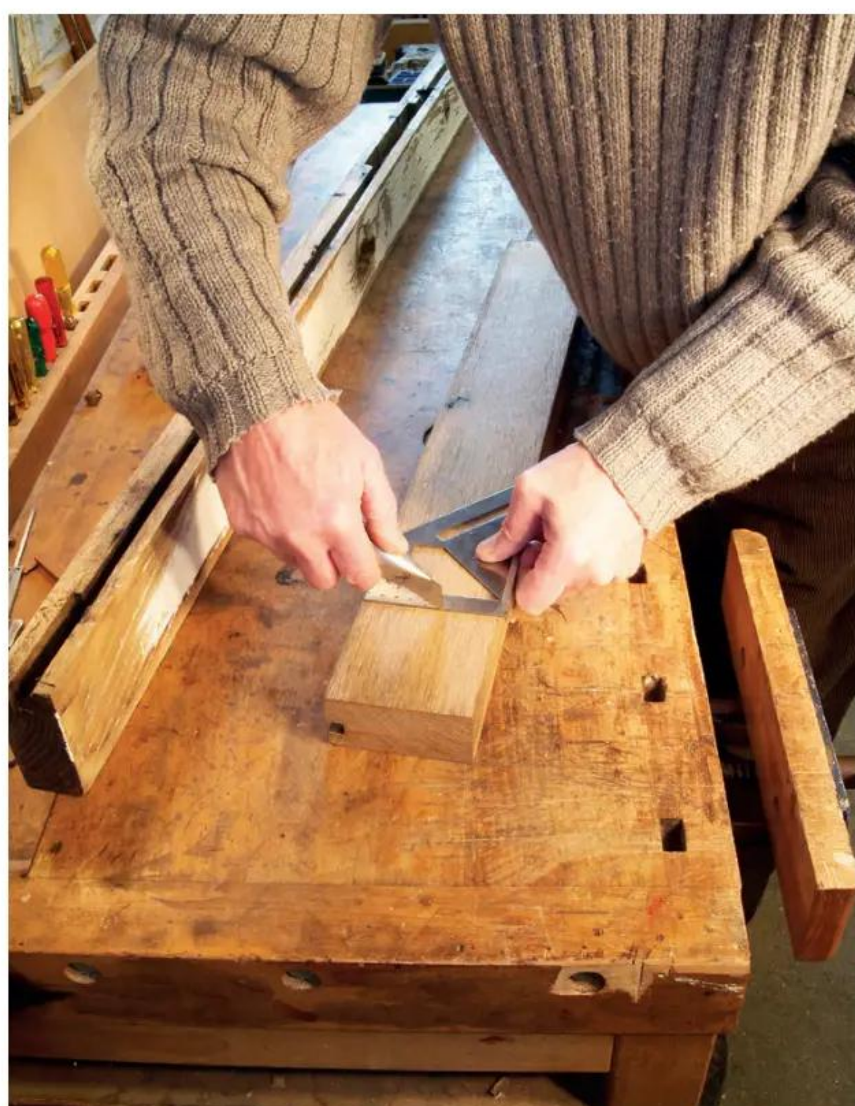
8 Offer the square up to the blade and run the line across the rail
