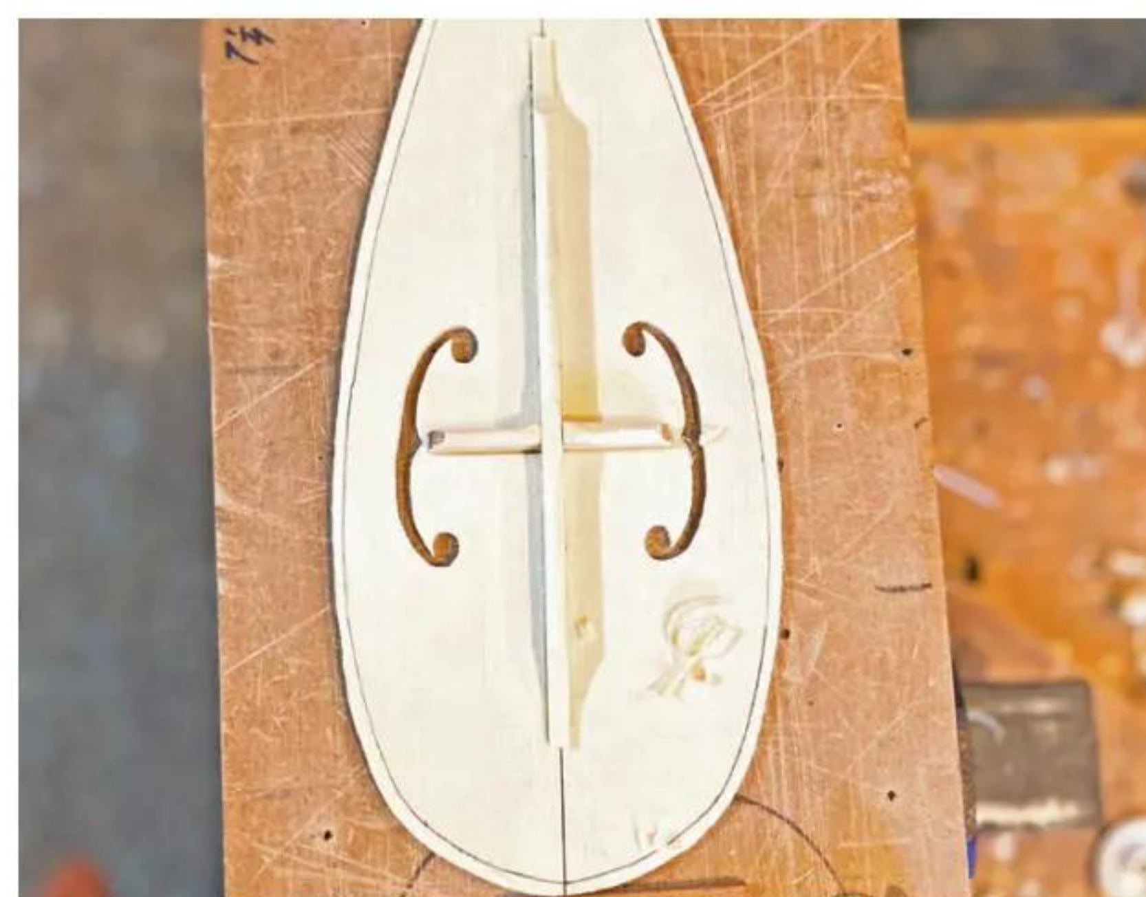
13 The soundboard once braced
