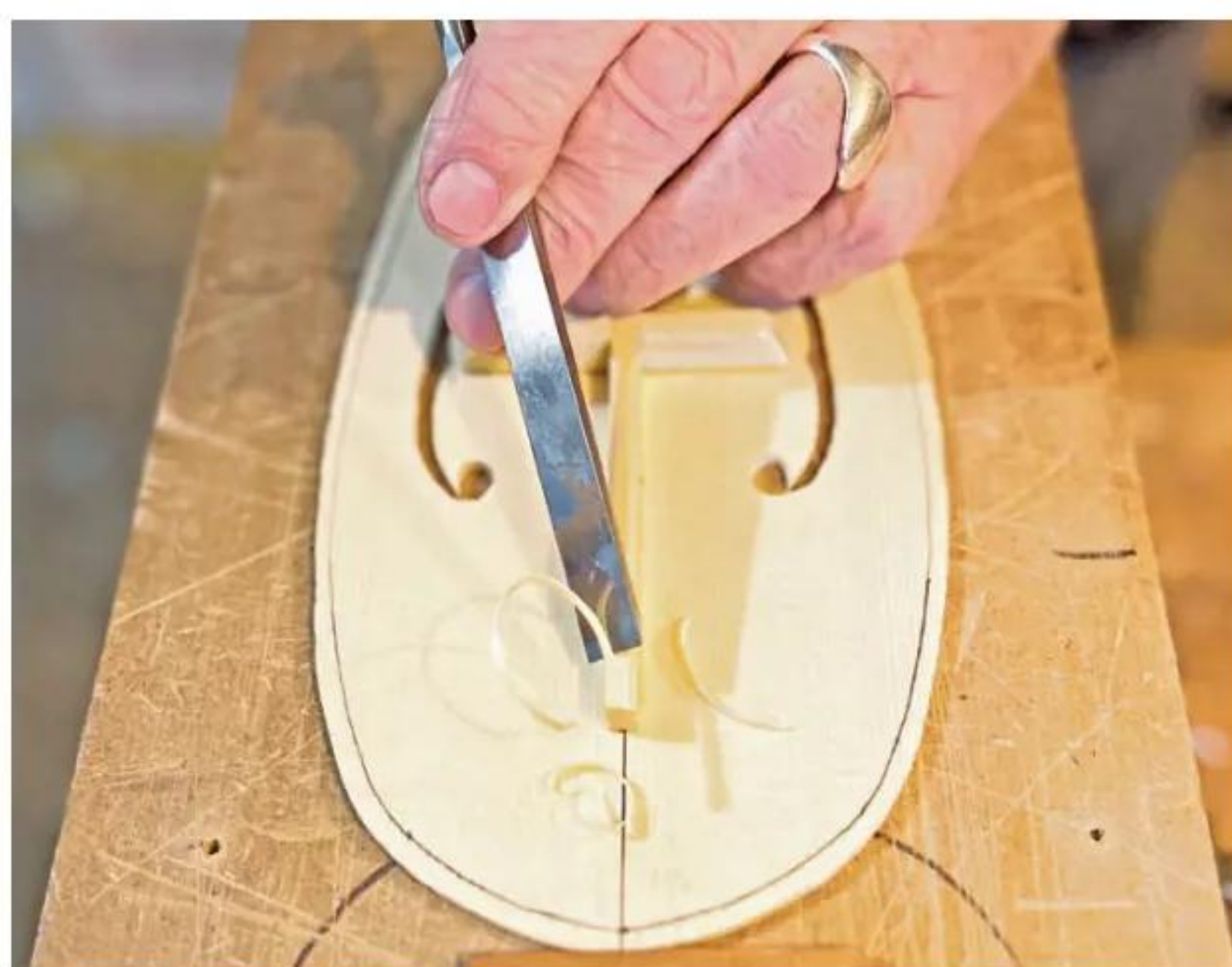
12 The front braces are scalloped and gabled
