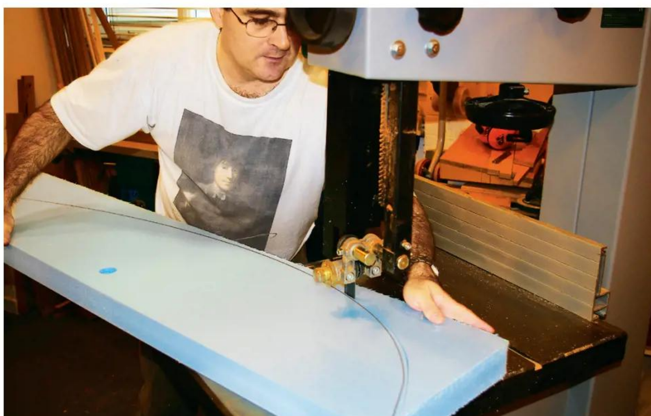
3 Cut out the blanks roughly to shape on the bandsaw...
