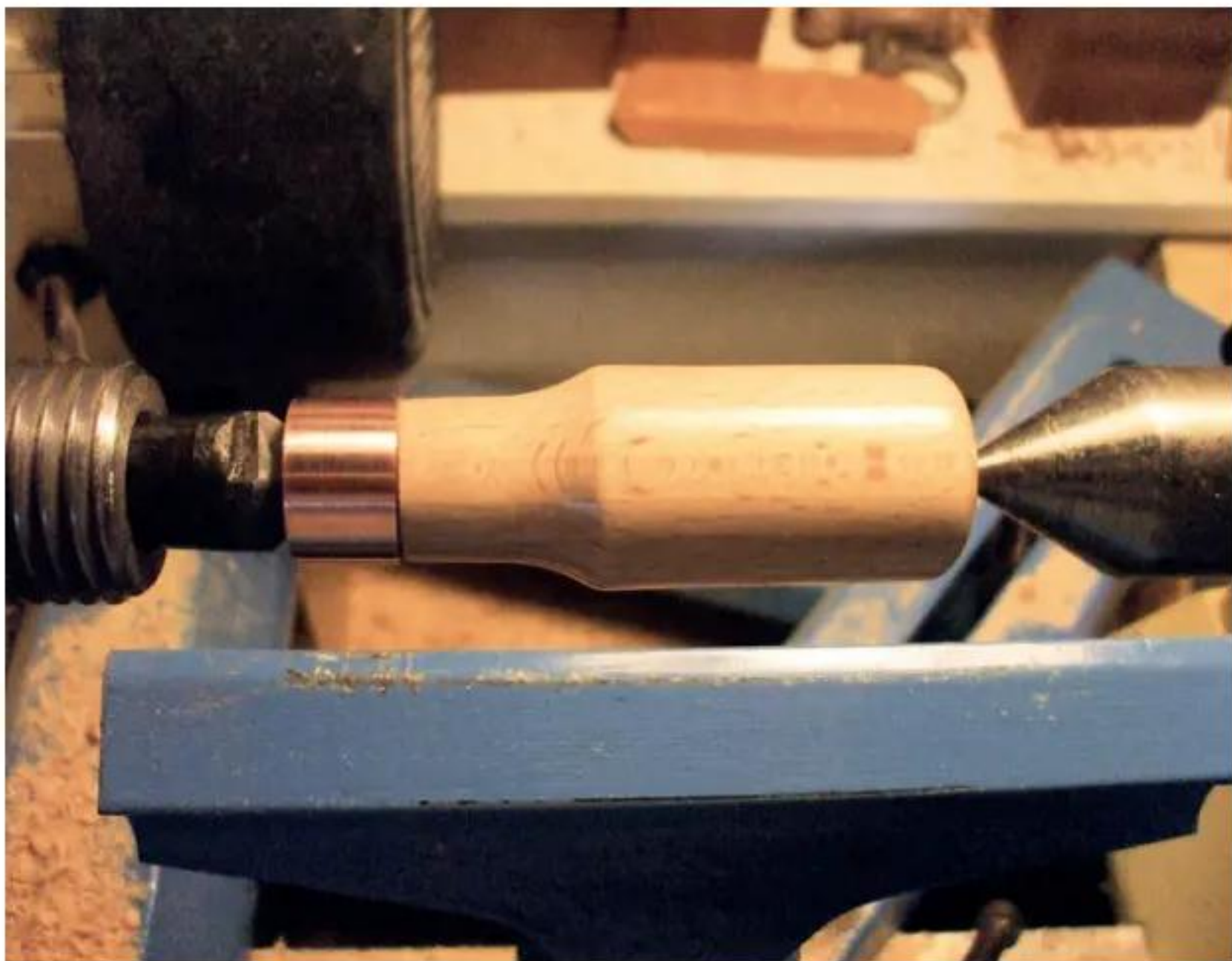
8 Glue the ferrule in place with epoxy adhesive and finish the handle
