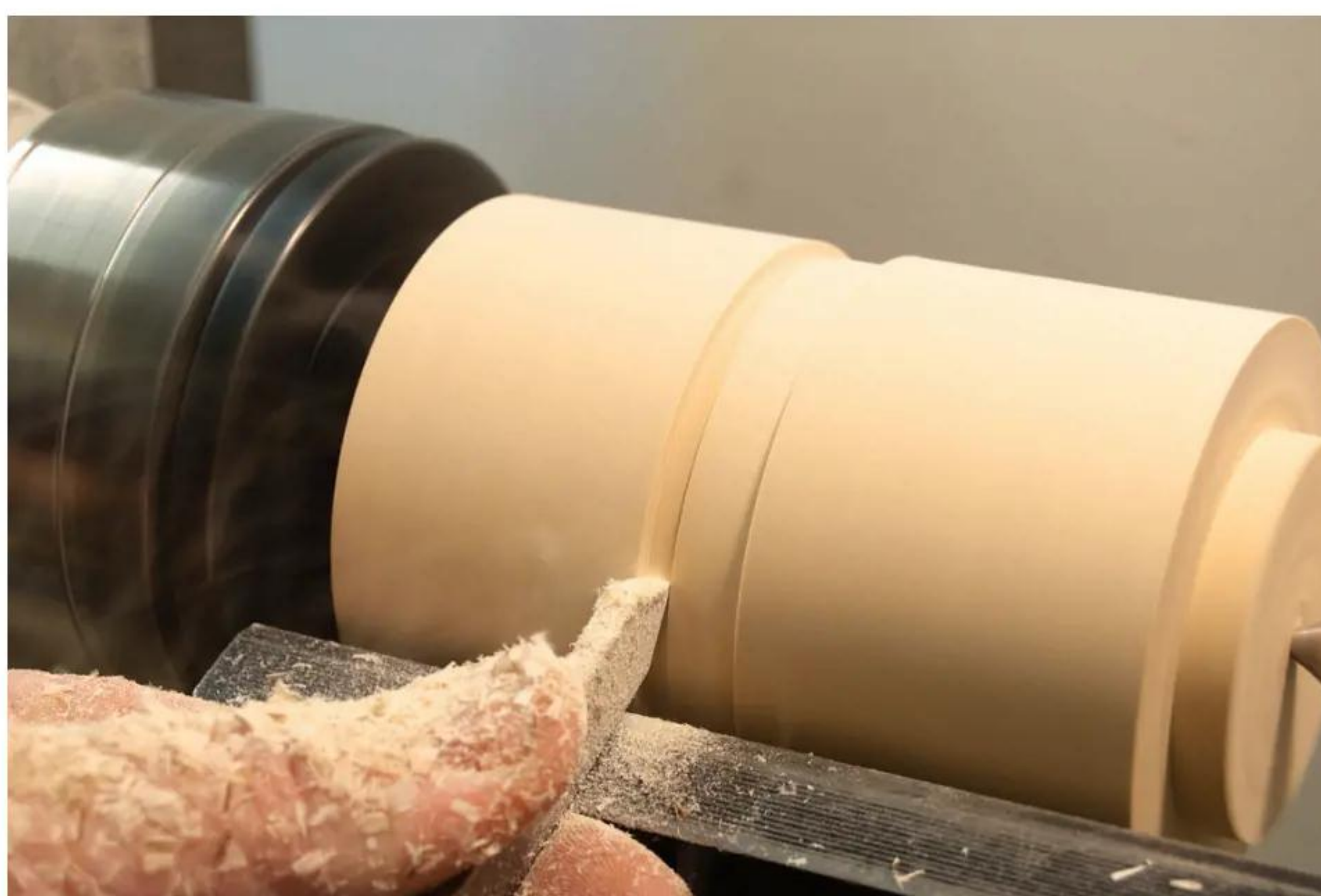
2 Use a parting tool to turn the spigot where the join between the lid and base is going to be...
