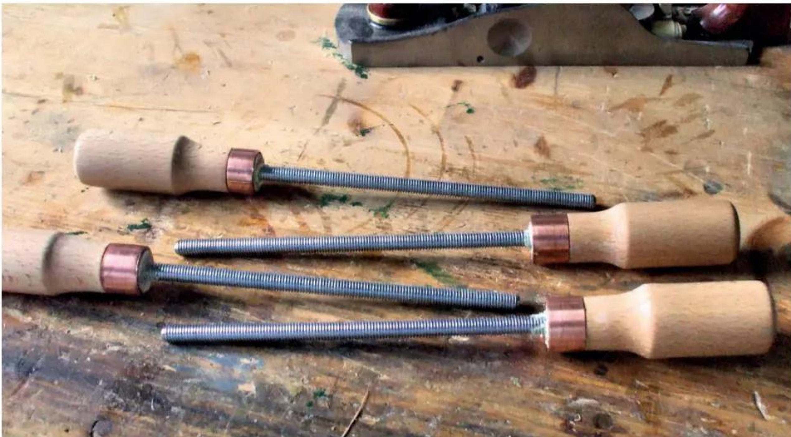
9 Cut the lengths of studding and glue them into the handle holes
