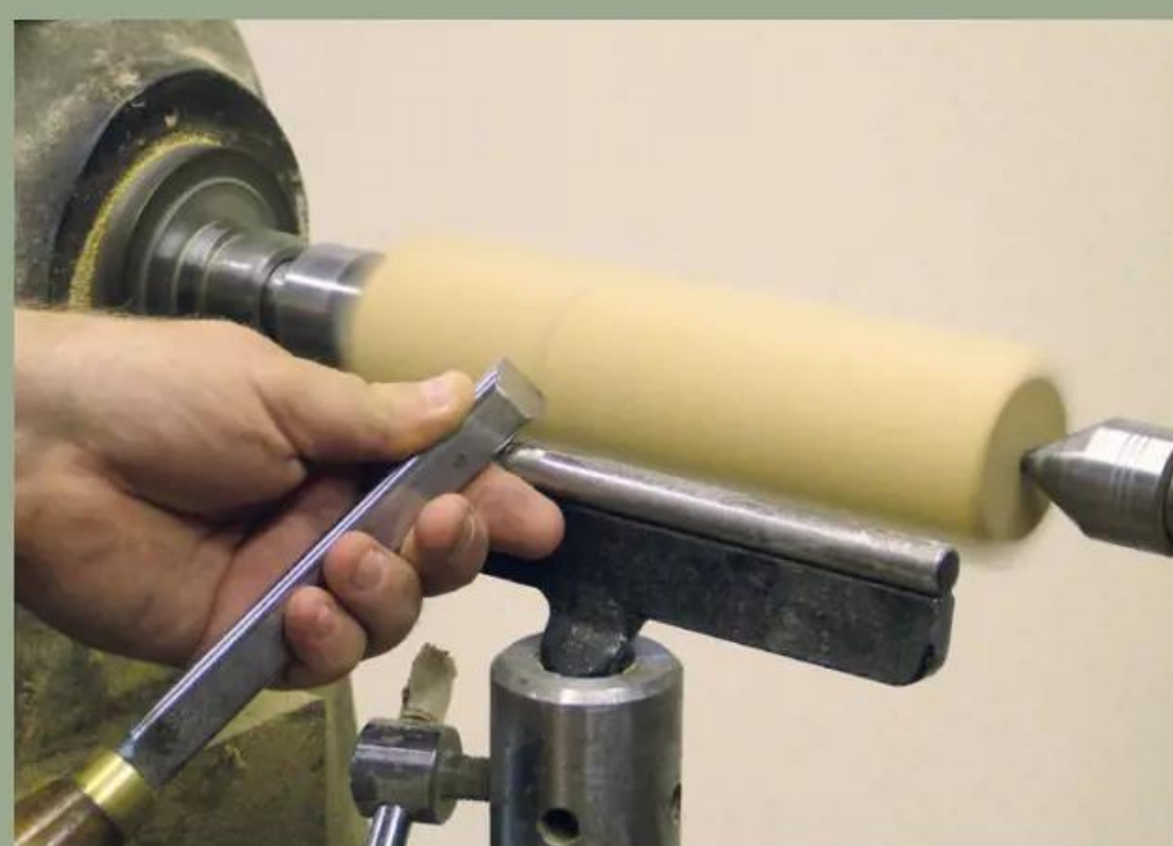
9 Secure the blank on the lathe and start to cut the pommel shape
