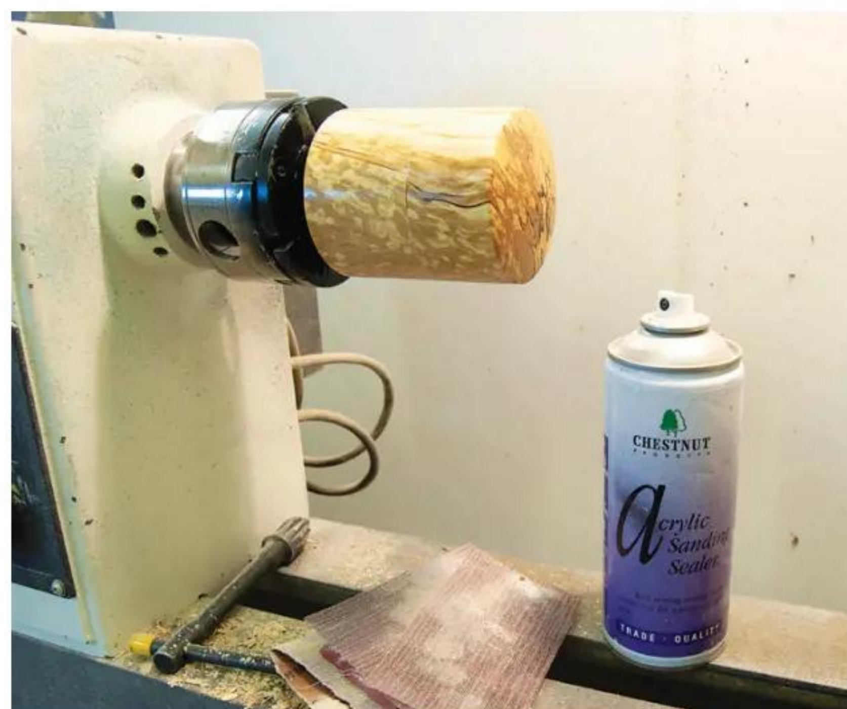
11 Due to its spalted nature, lots of sanding sealer is required to seal the wood
