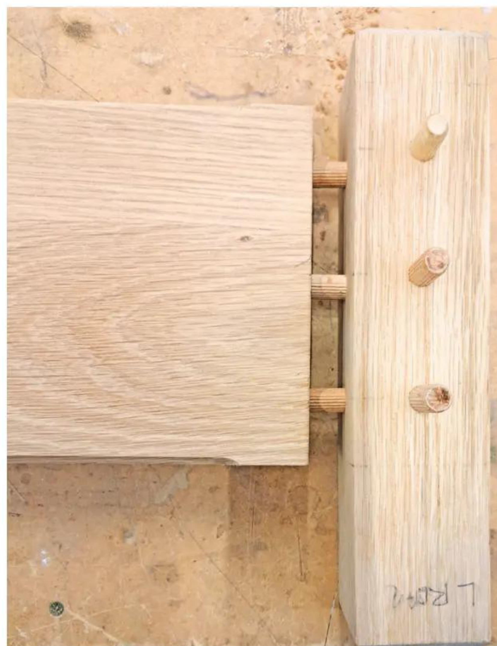
2 Remaining joints made use of a dowel construction
