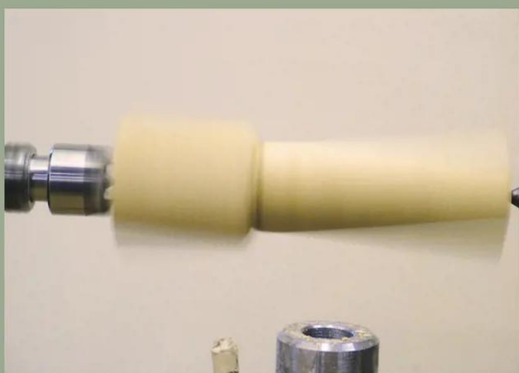
17 Offset the leg using the two other centres and look for the ghosting
