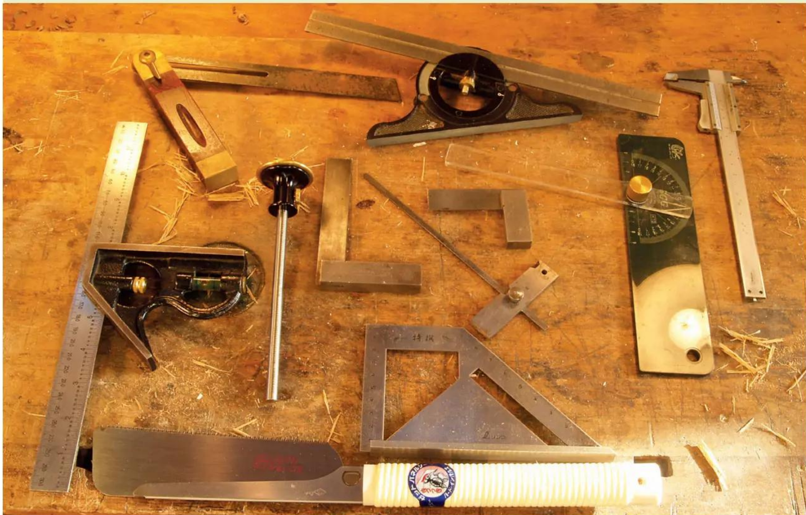
4 A wheel gauge is expensive but easier to set than a pin gauge
