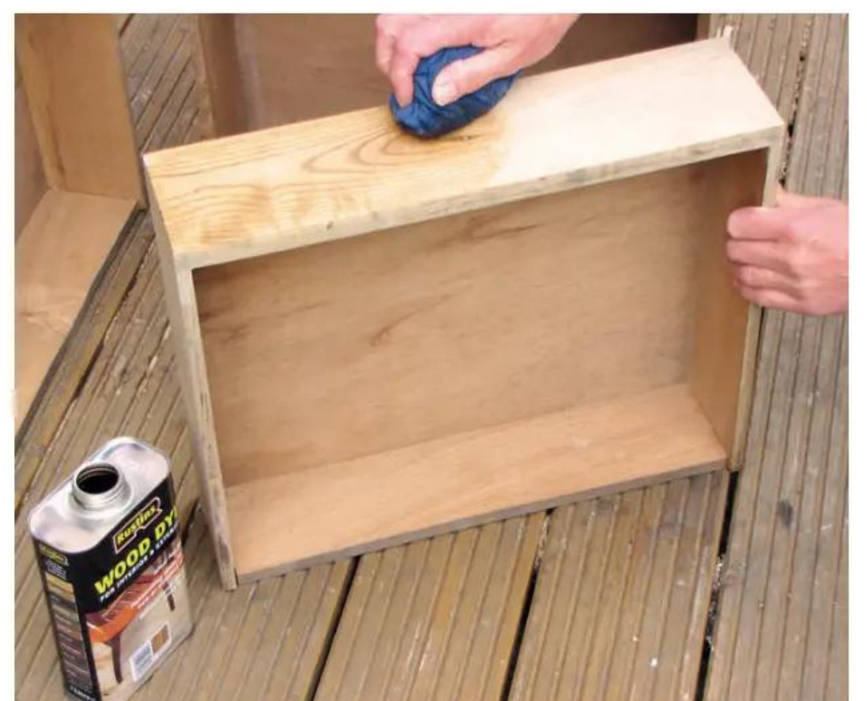
11 Lightly sand, then stain the wood to restore the colour; to check this, it's advisable to carry out an initial test on the back of a drawer
