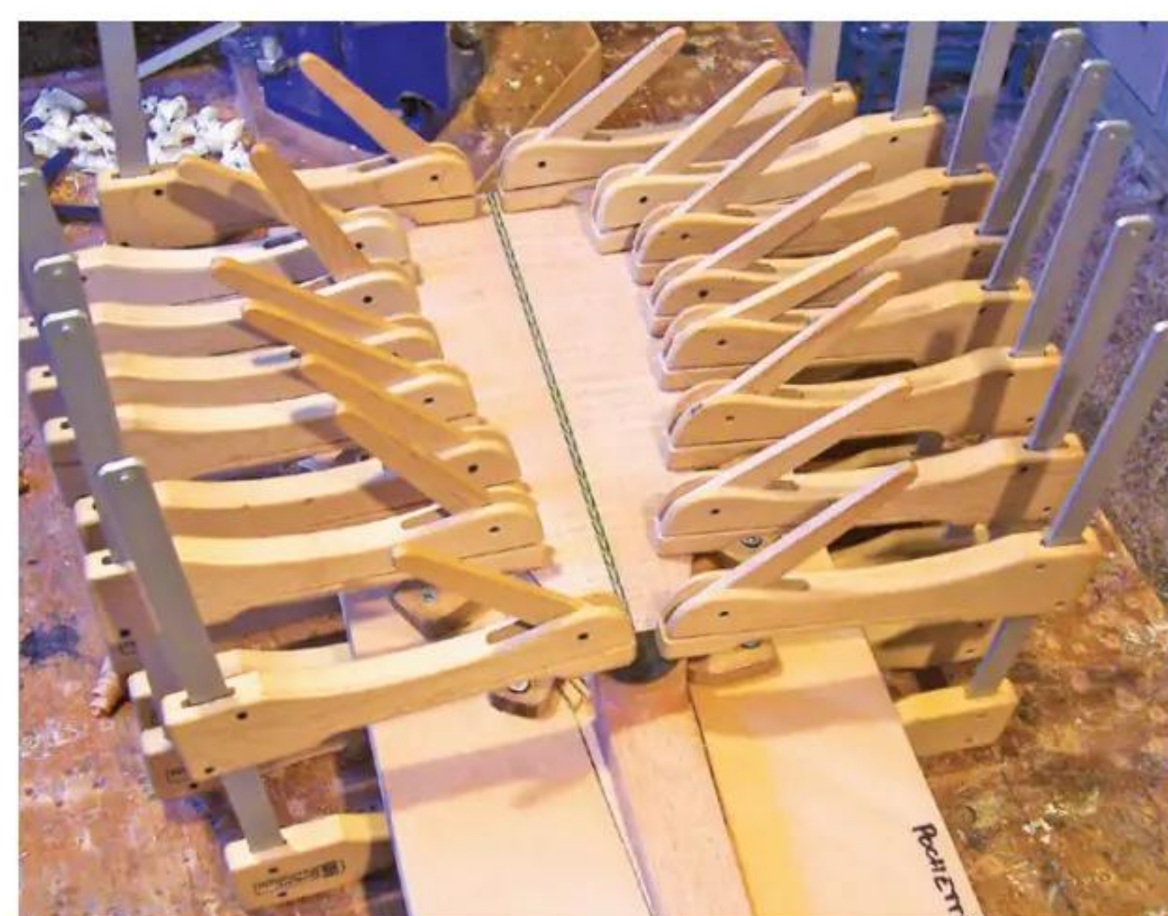
19 The back is pinned into place with cam clamps
