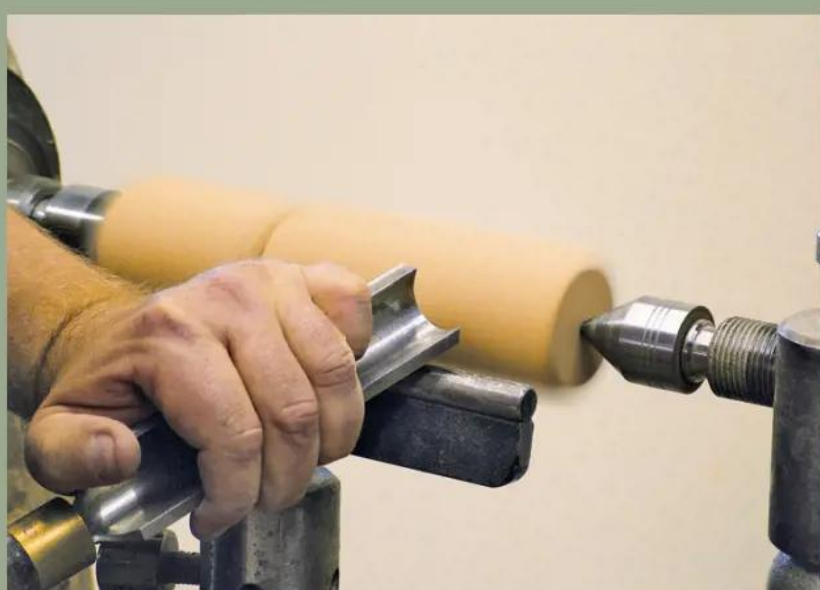
13 Use a spindle roughing gouge to turn the remaining leg to round
