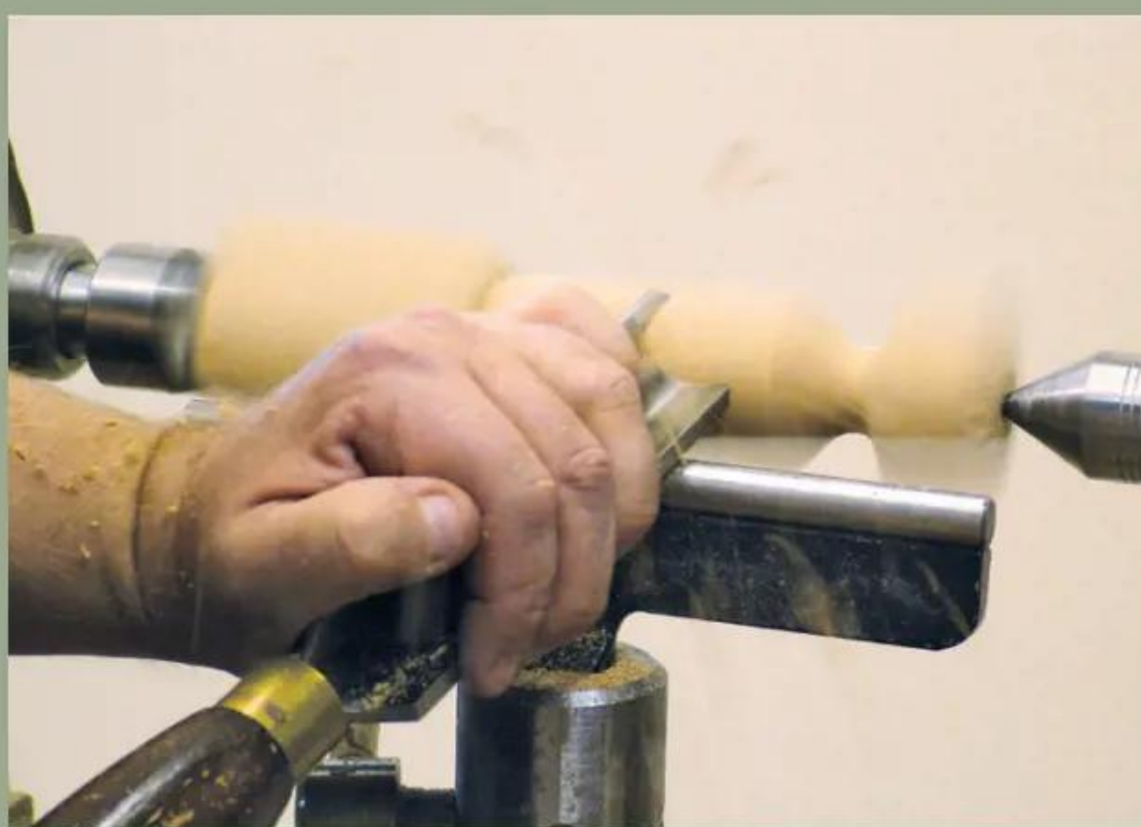
21 Remove ghosting on the leg with the spindle roughing gouge
