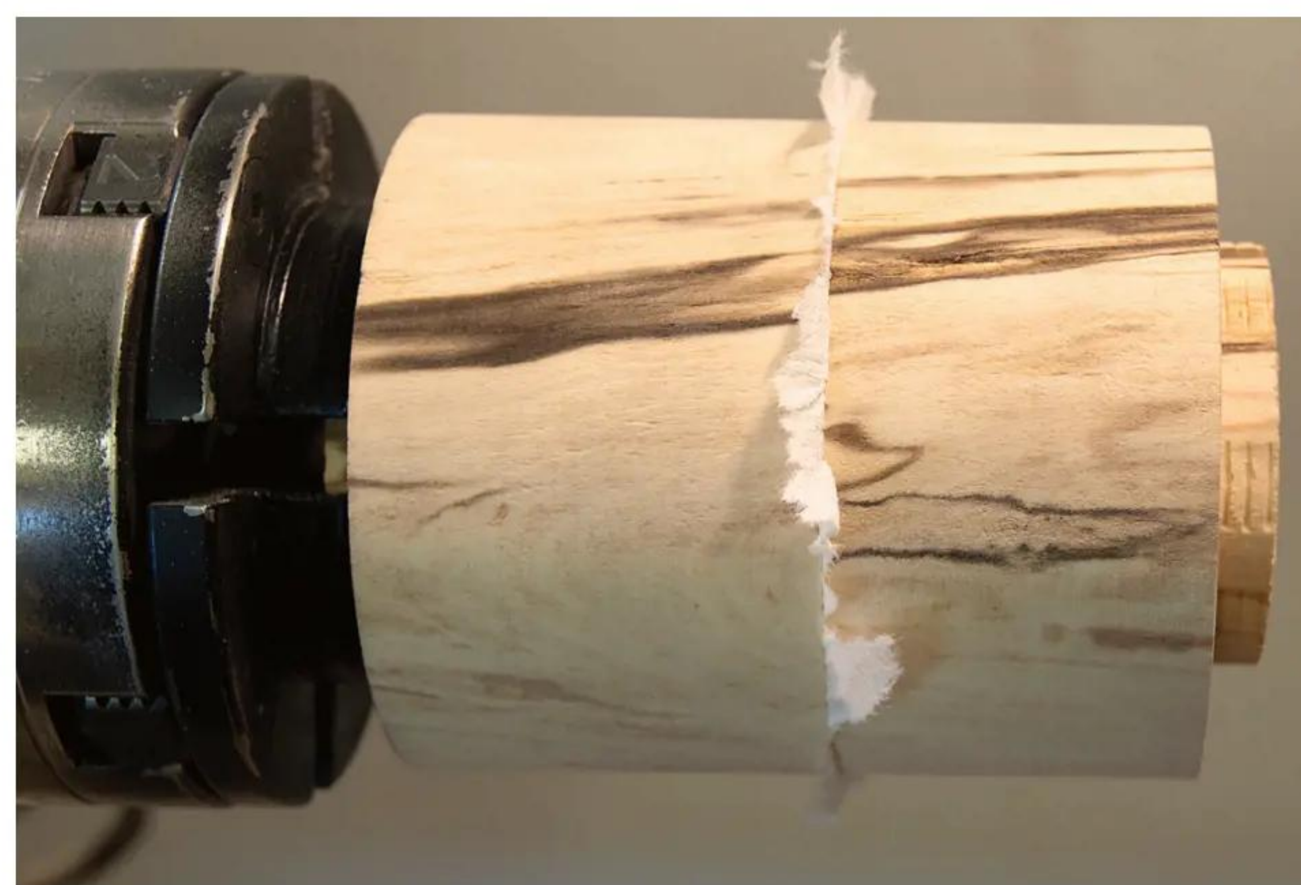
8 A piece of paper towel will increase the friction fit, but if you use too much, you'll experience vibration later
