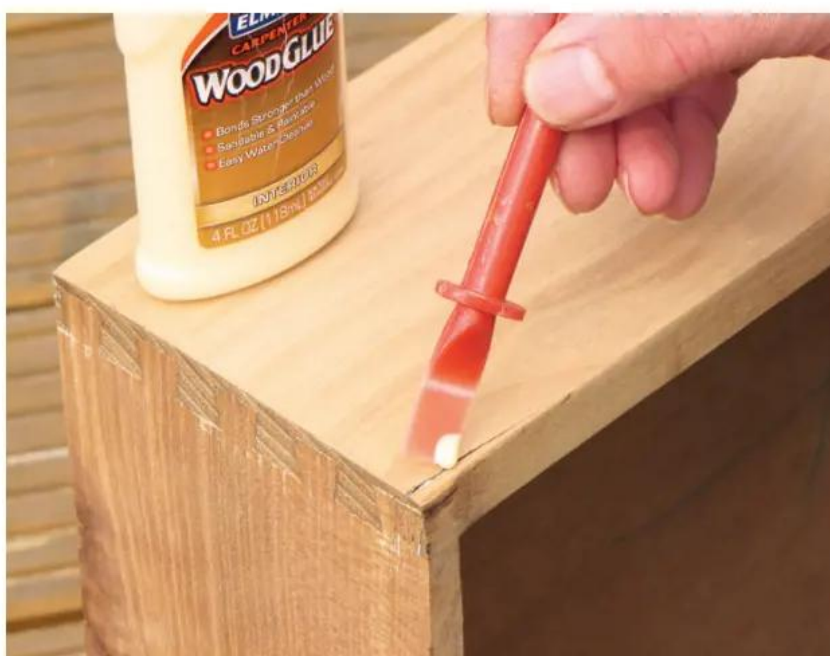
7 Glue and cramp any split drawer components or loose edges; sand once the glue has dried
