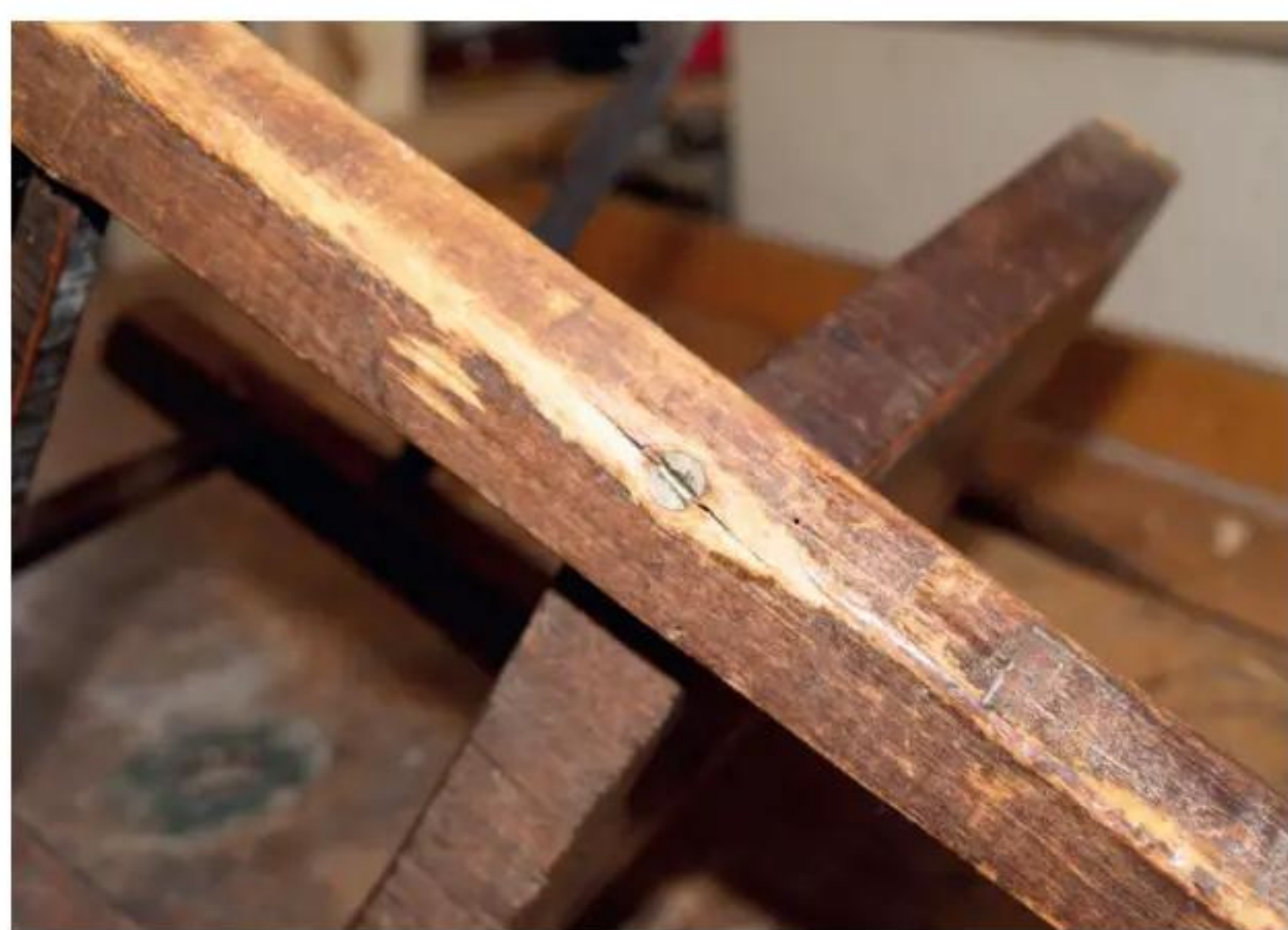
4 ... but had been repaired with screws
