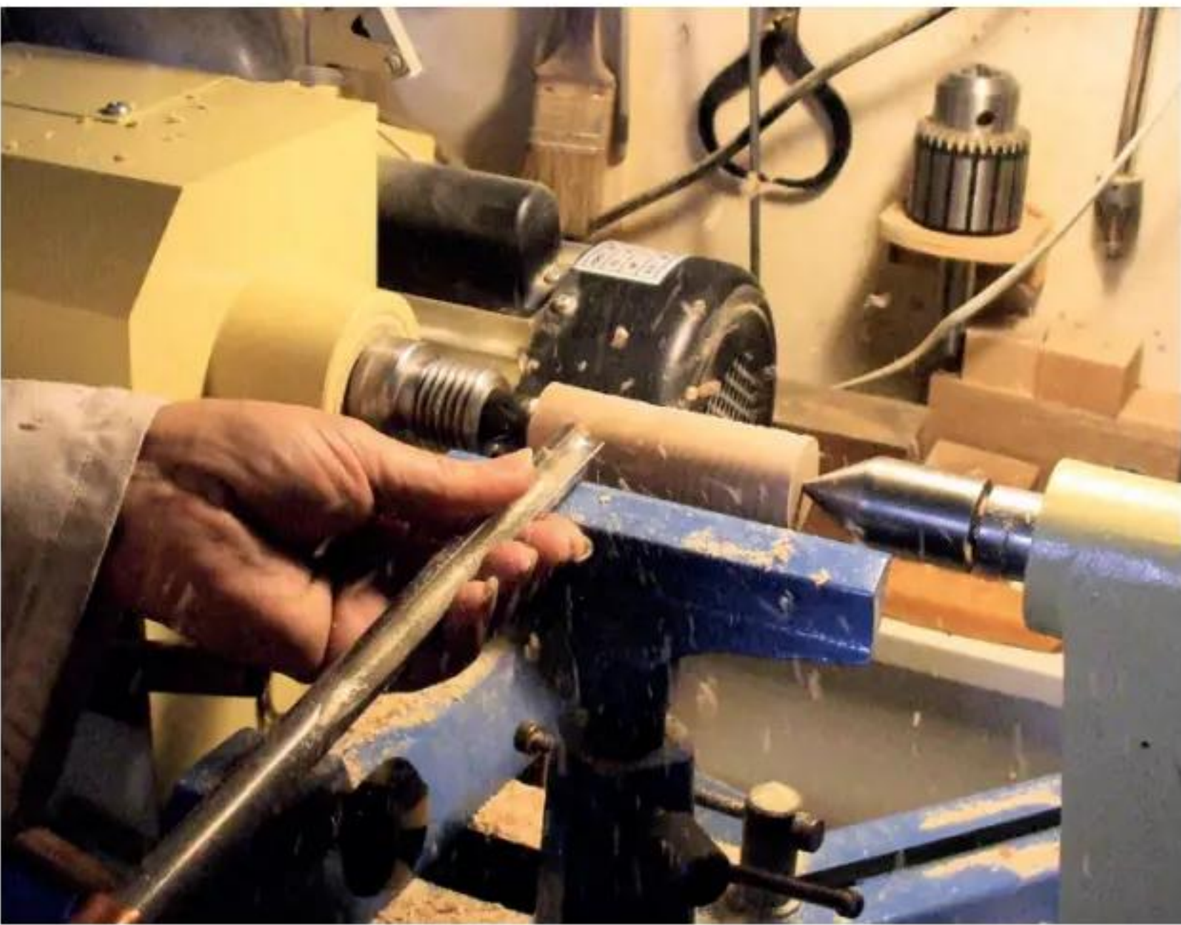
7 Turn each handle blank down to a cylinder and decorate it to taste
