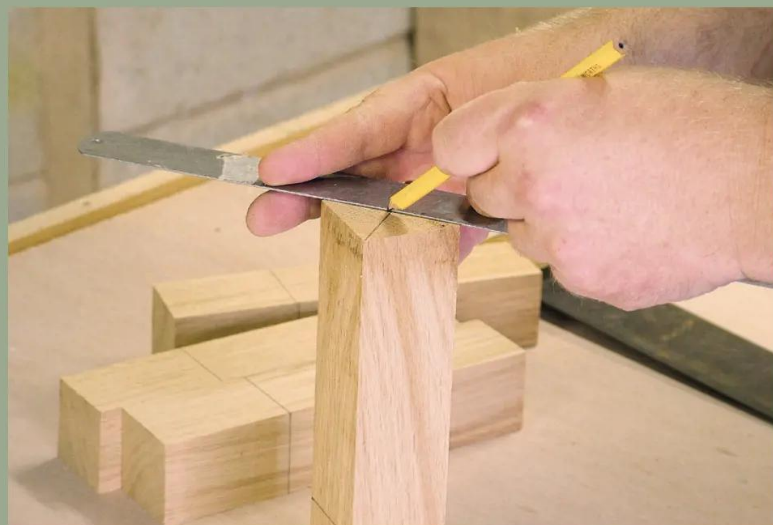
7 Mark the centre of each end of the blanks by drawing diagonals on it
