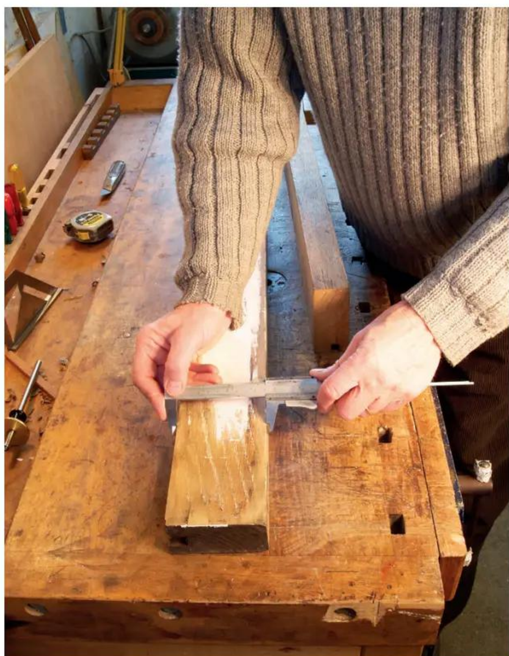
5 Vernier callipers are a must if you're using odd timber sizes
