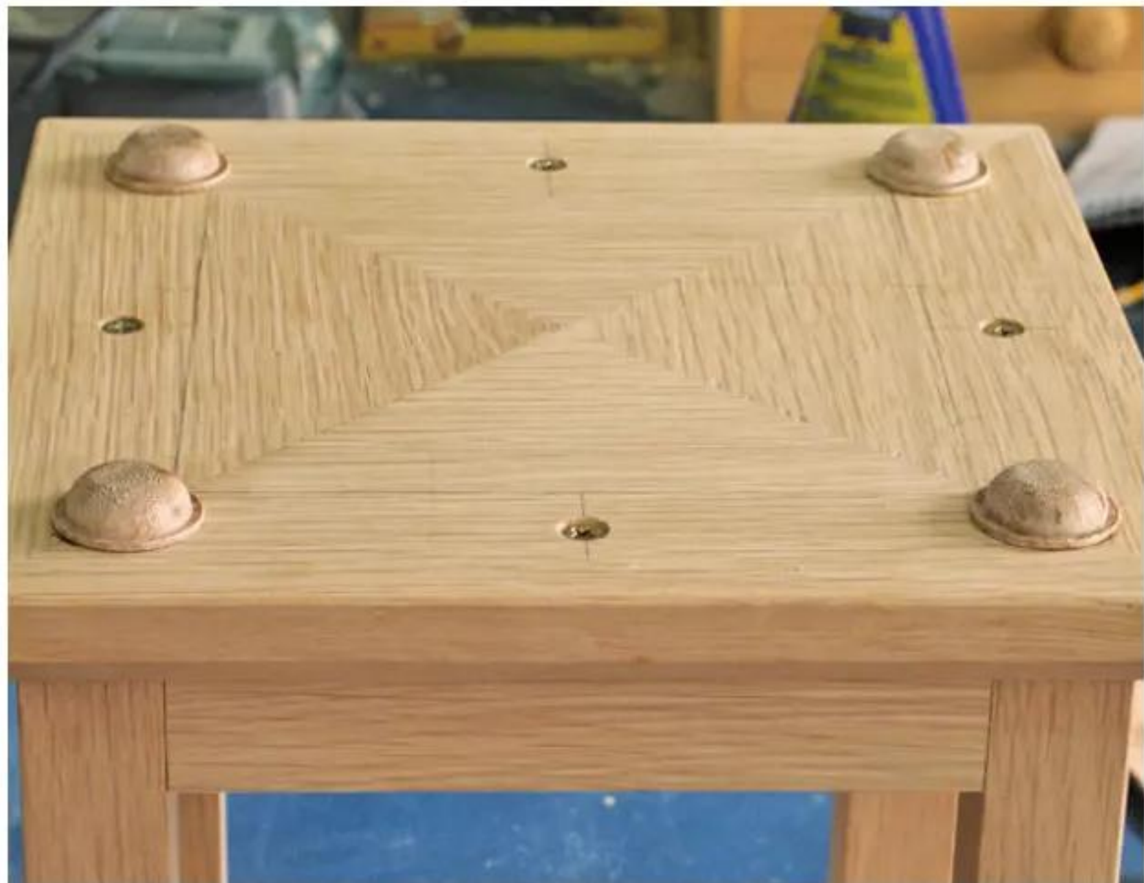
20 The end can then be cut off on the bandsaw to produce a foot, which can now be glued to the lantern's underside
