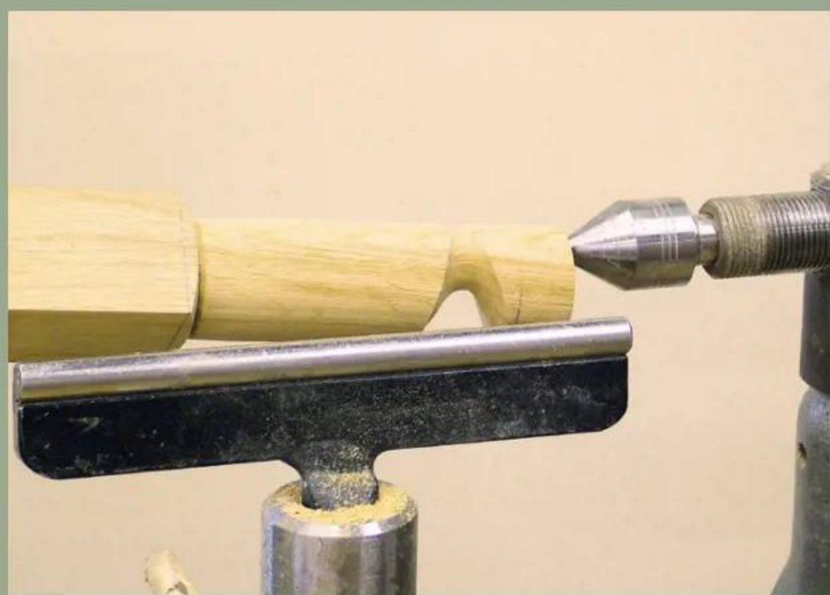
20 Ensure the cove's depth just cuts all the way round the leg
