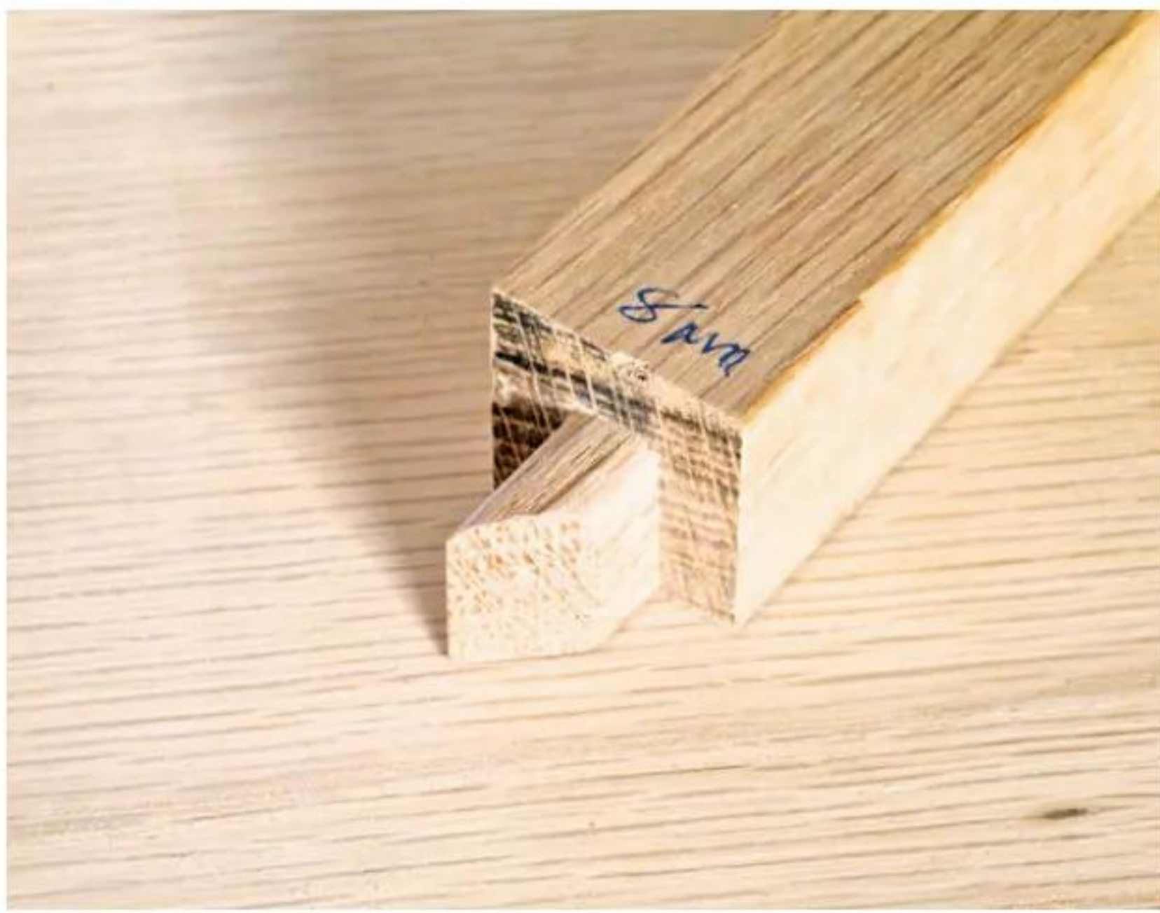
7 The tenons needed to be cut at 45° on their ends; this can be completed using either a small bandsaw, which is preferable, or a fine tenon saw
