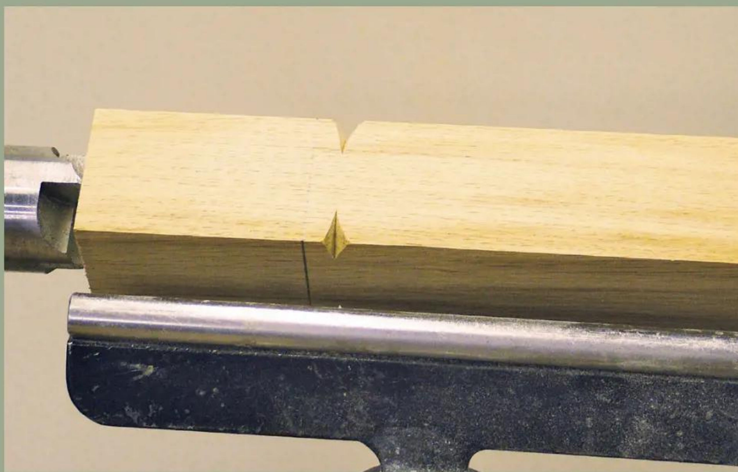
11 Cut the left and right side of the 'V' alternately to create this shape
