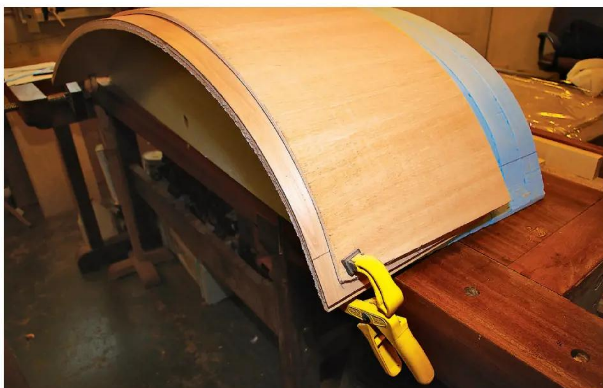
10 Mark out the legs using a template made from a spare piece of bendy ply...
