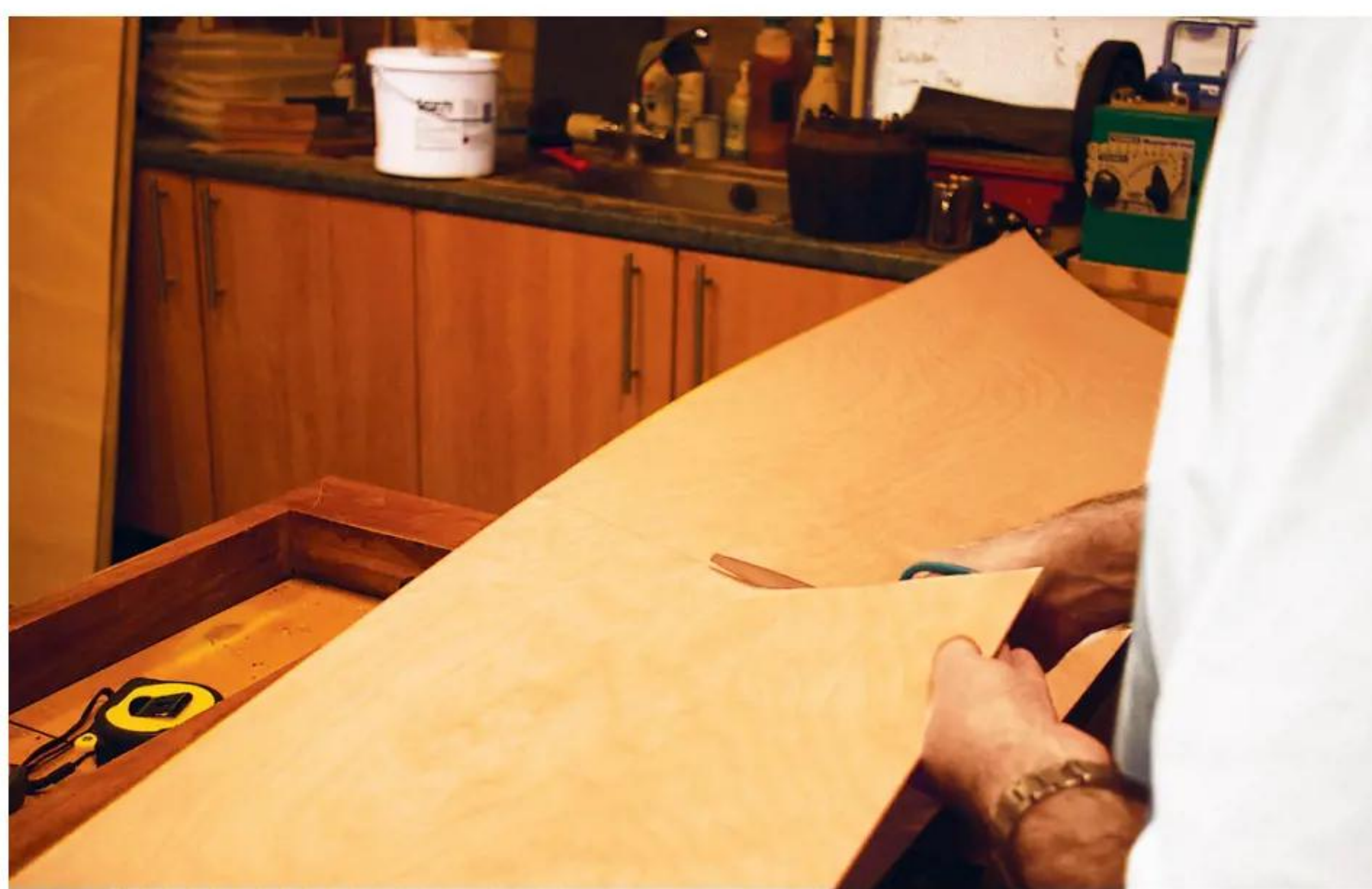
8 Face the bendy ply with aero-ply to provide a smooth substrate for the veneer
