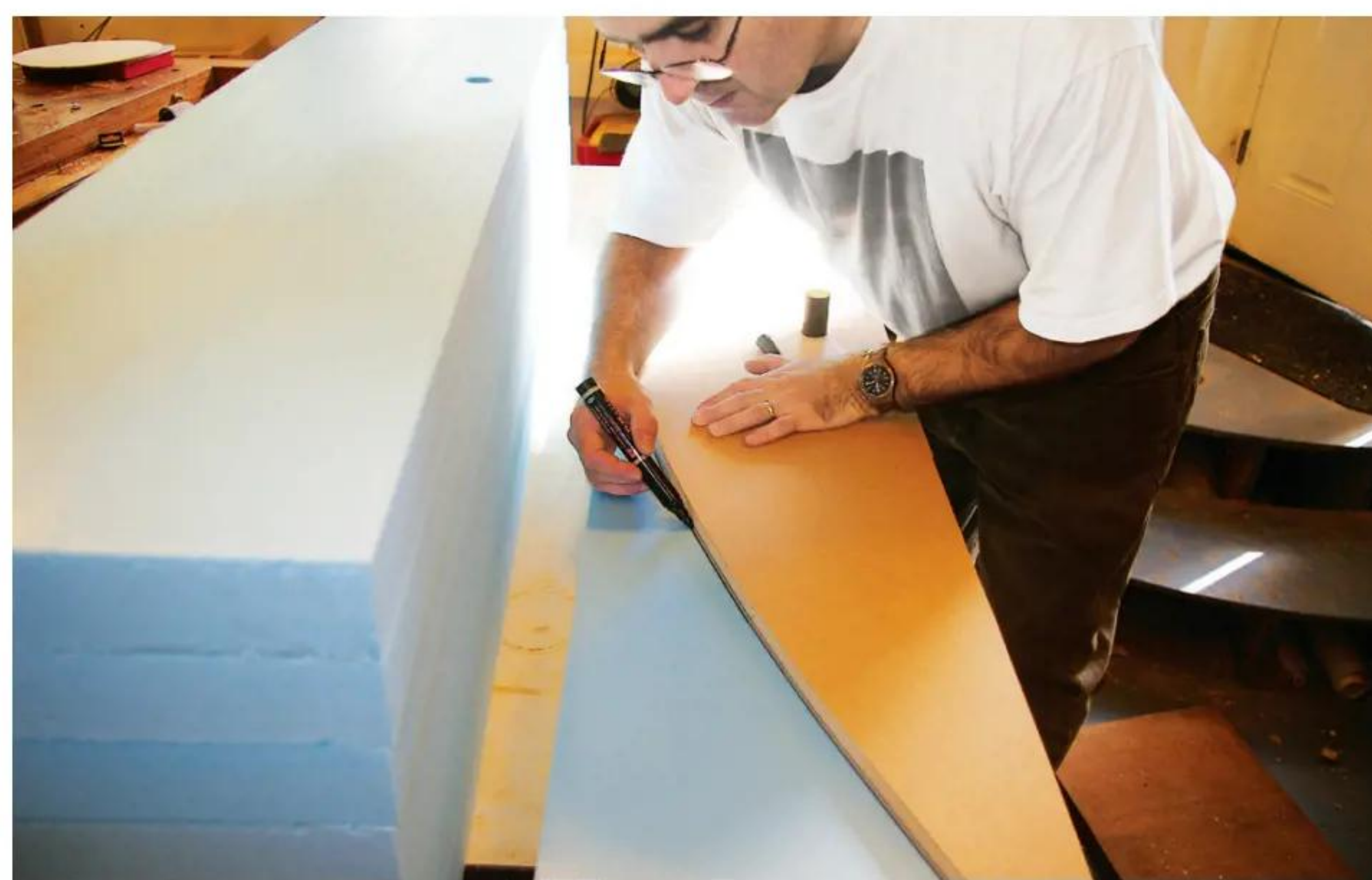
2 ... transfer the template's outline with a marker pen
