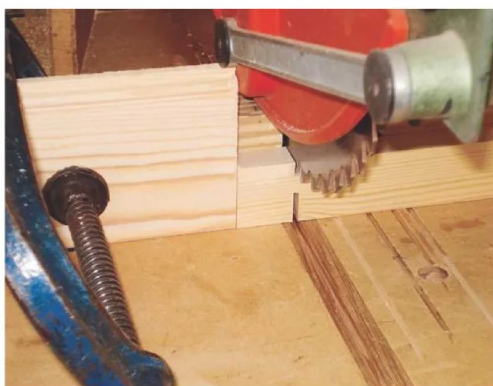
13 More machinery, this time to cut tenon shoulders on the rails...
