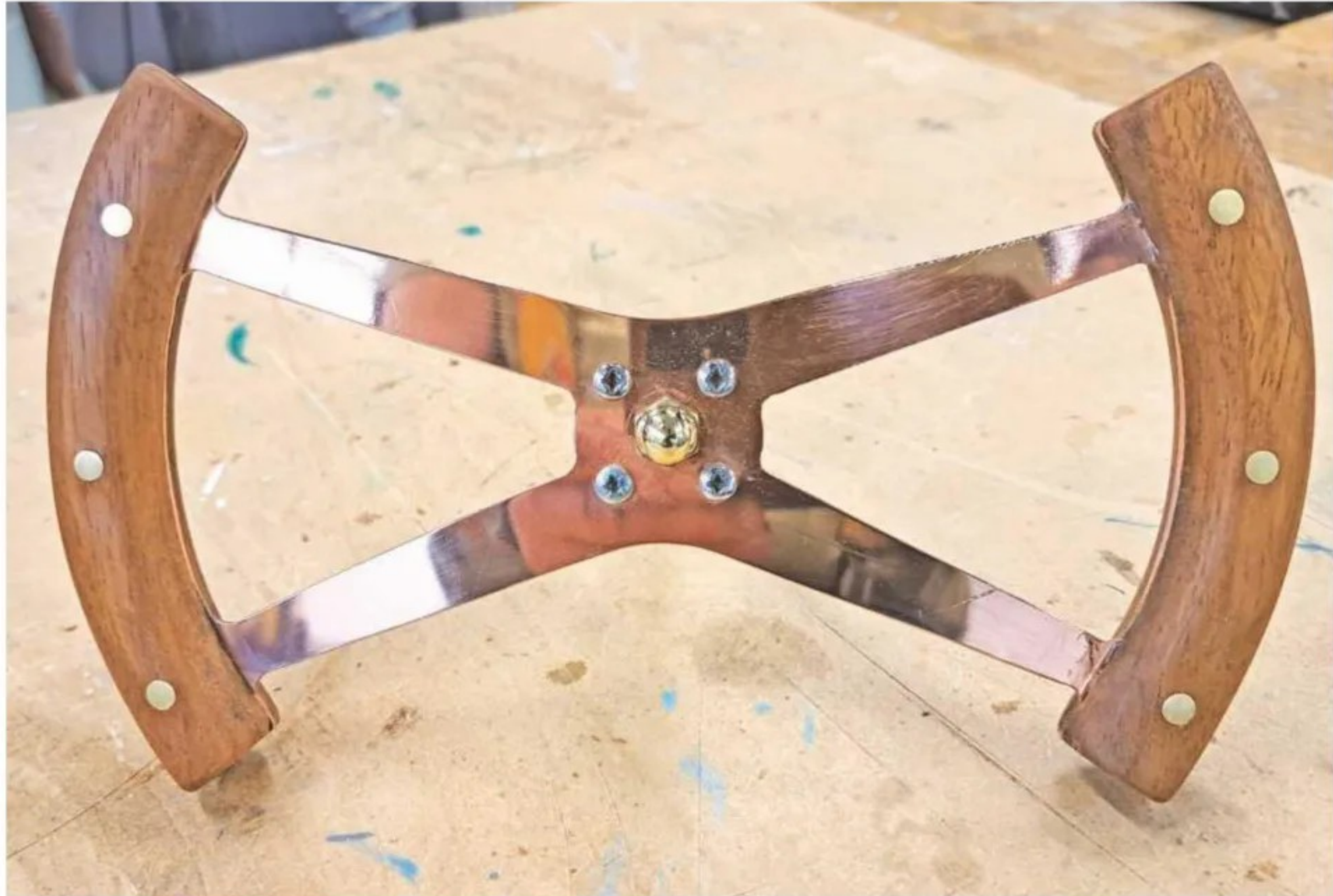
18 The steering wheel made use of some left-over copper sheet
