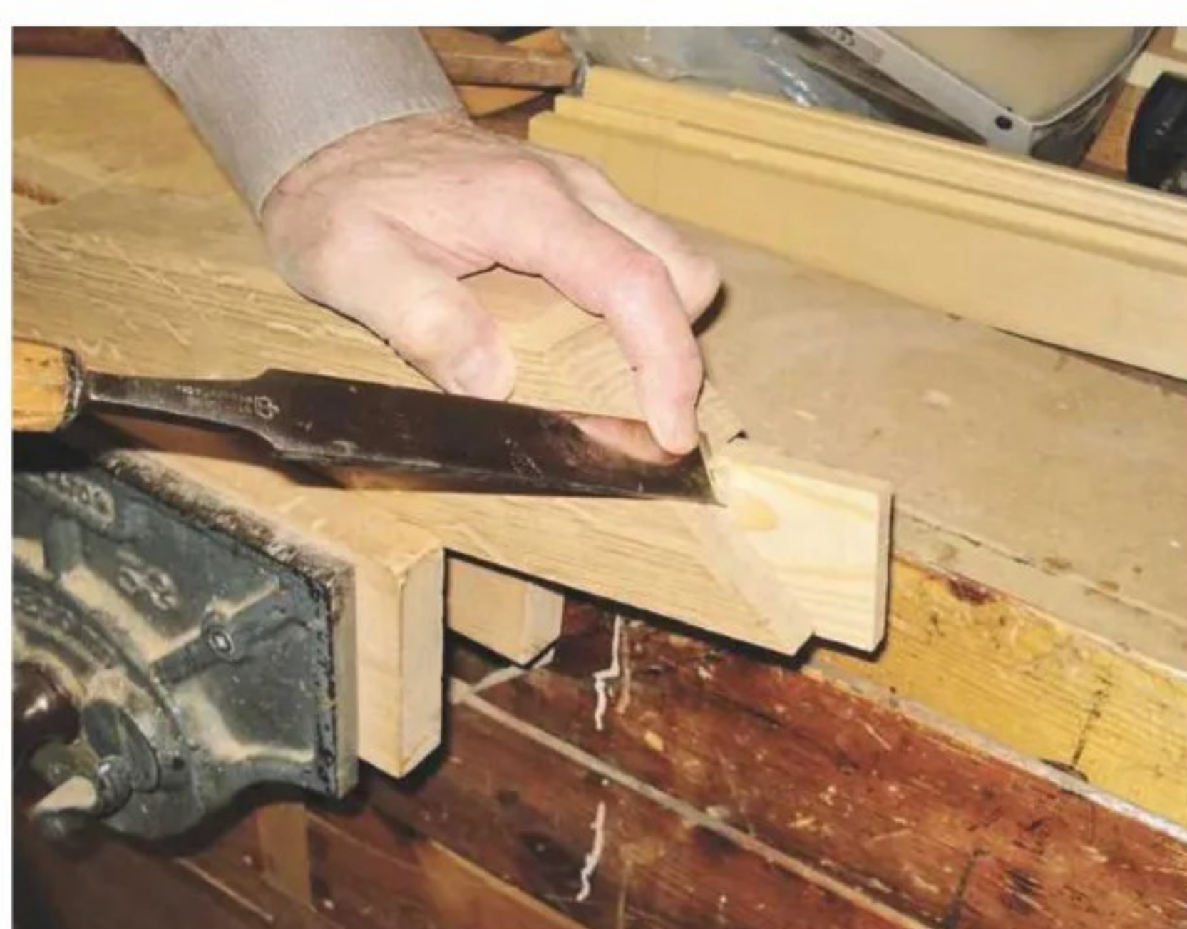
16 ... when cutting an ovolo profile on the window rails
