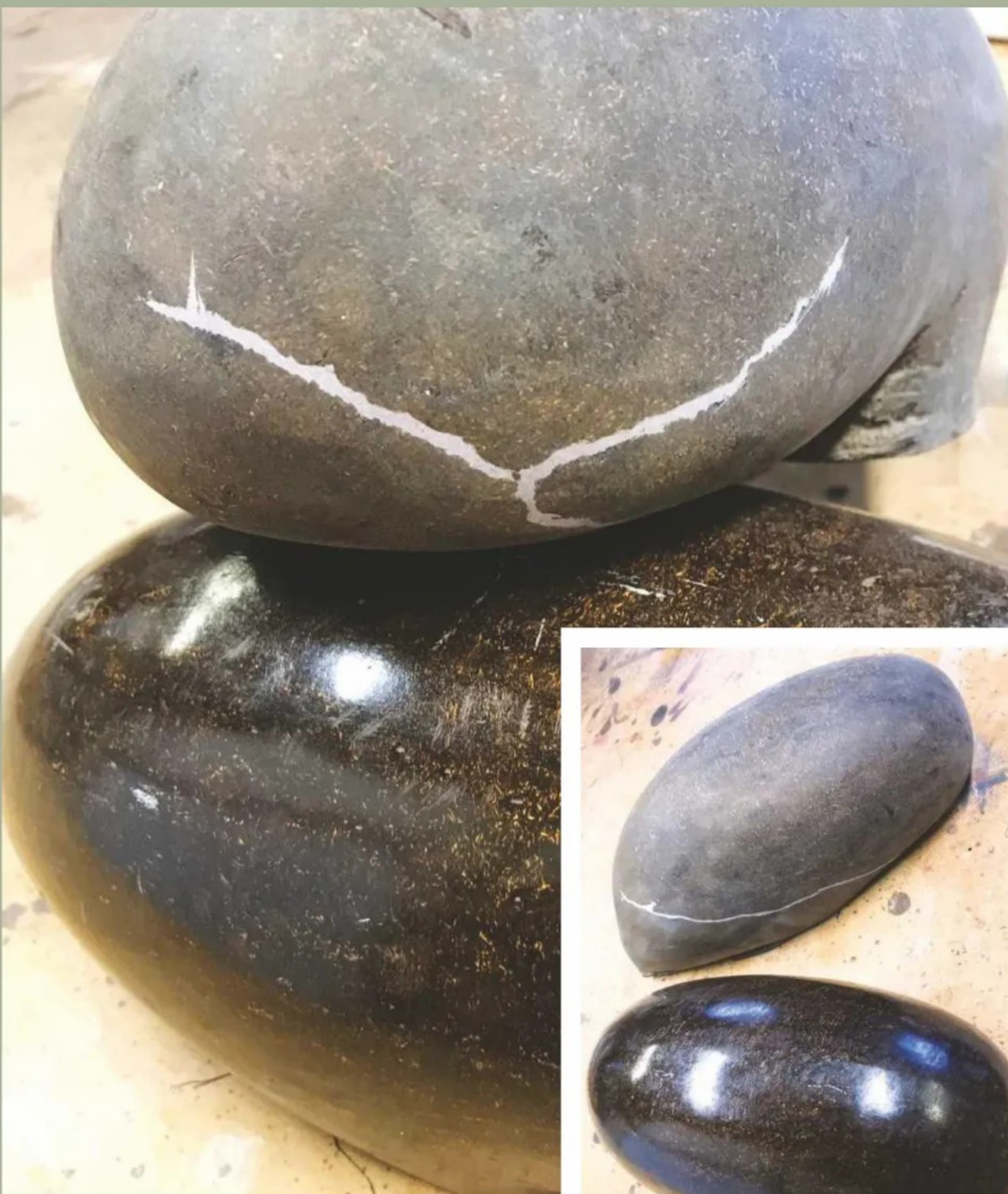
7 & 8 If anyone has ever tried to glue up and hold something like this, you'll know it's not easy! I used PVA here, and plenty of it. In anticipation, I'd torn off some short lengths of masking tape and had those to hand. I jiggled the two halves together to ensure there was a good bond and tried to line them up. Clasp the pod between my knees, I popped the first bit of tape on, readjusted the joint, then got some more on as quickly as possible. Reasonably happy with progress so far, I then wrapped long lengths of masking tape all round, double checked the alignment, and left well alone so the adhesive could cure
