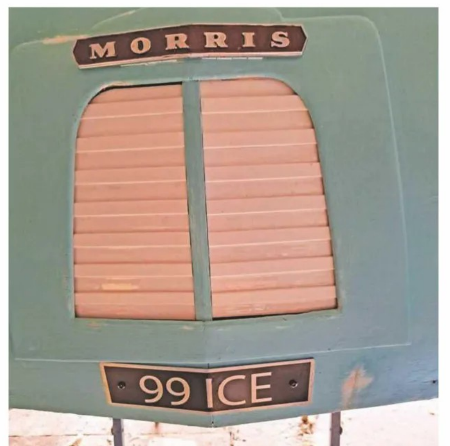
11 The radiator grille, vacuum formed in two halves
