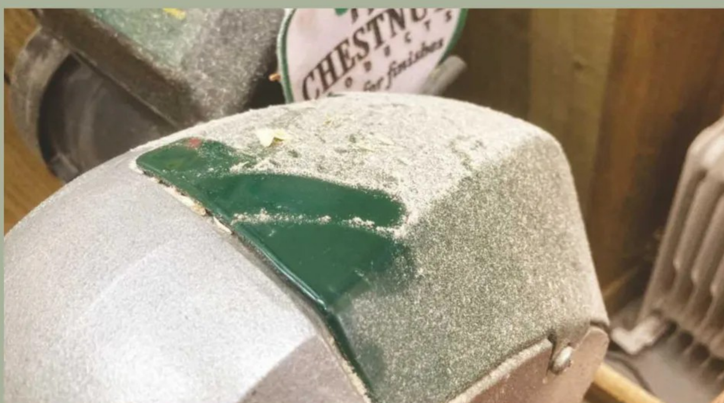
23 It's amazing how much dust is generated from both turning and sanding; that's why I wear a full-face respirator, have a CamVac running when sanding and also use an AC400 fine filter
