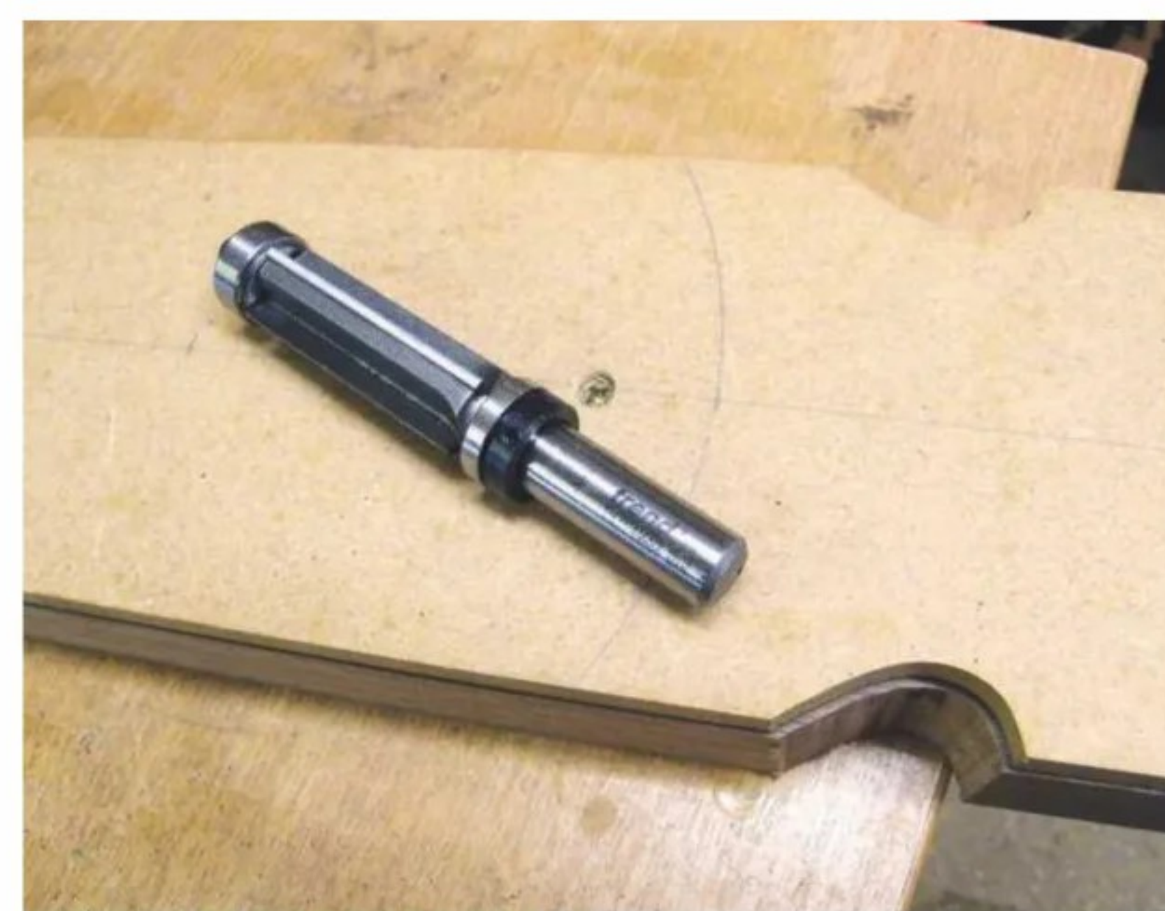
6 The double-ended bearing trimmer has four blades rather than two
