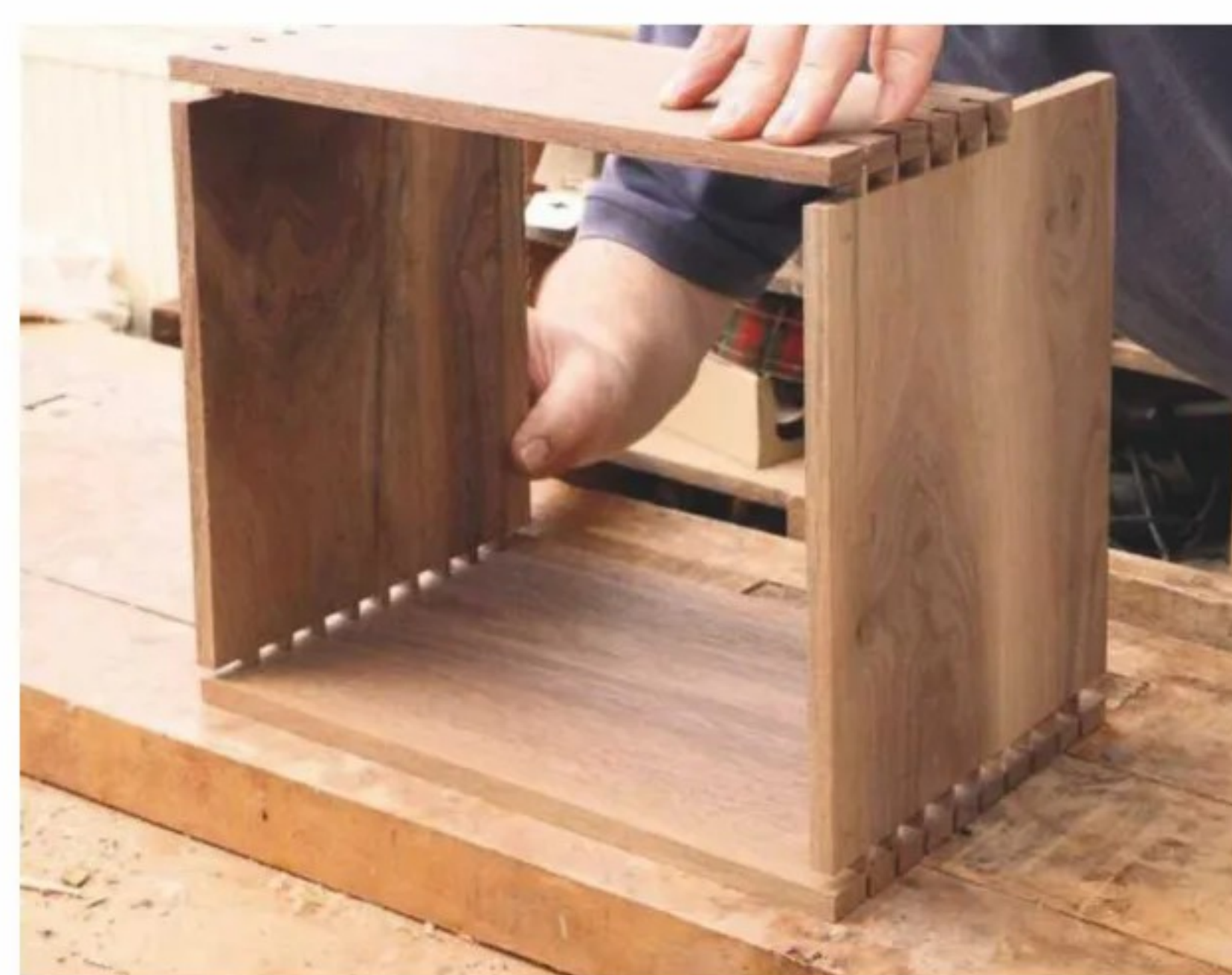
2 This compartmentalised case has dovetail joints cut on the side, front and back panels
