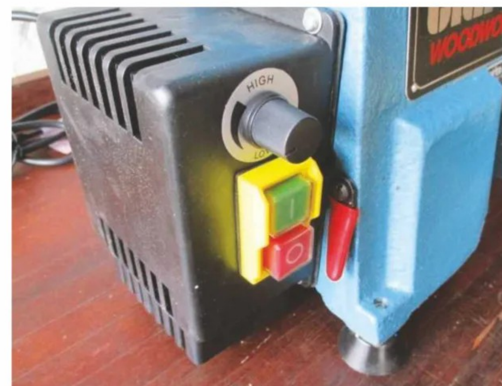
Lever down to lock in place
