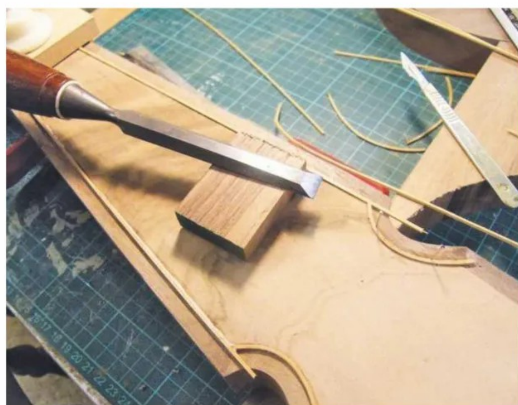
11 Glue and pin the stringing in place against the rebate's inner edge
