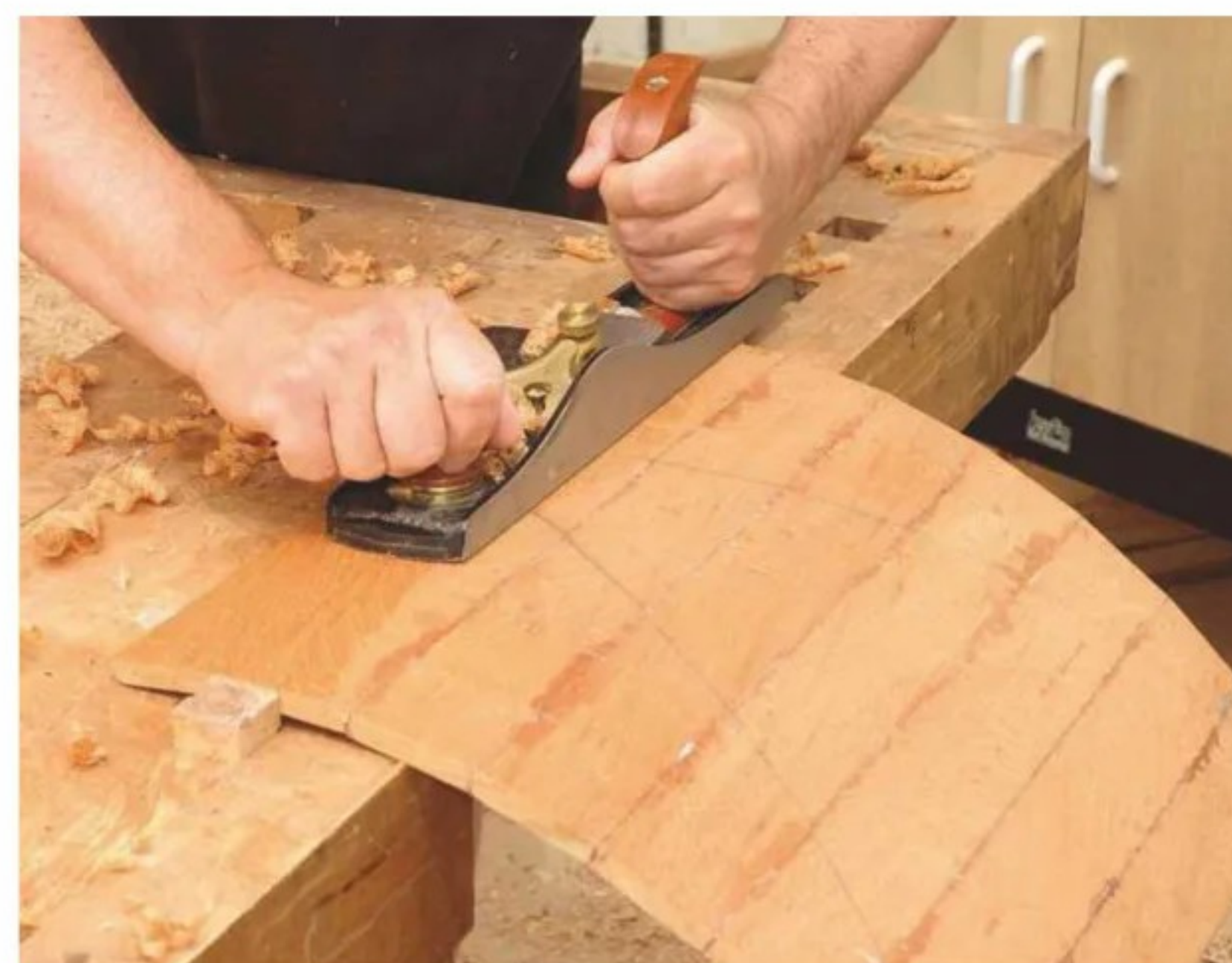
5 This arched box lid is 'coopered' with a series of narrow, flat sections, then the ridges are planed away to 'fair' the curve
