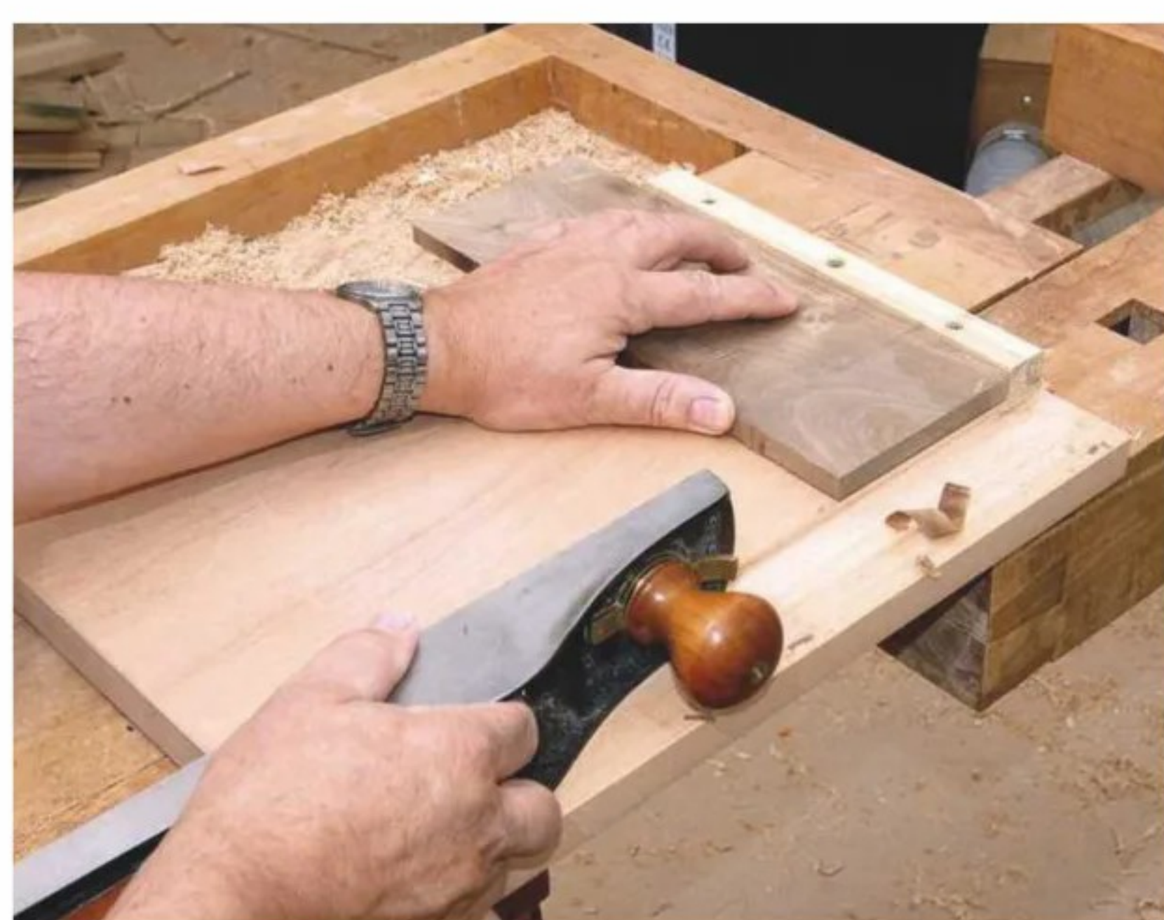
1 Using a shooting board to guide the block plane, in order to trim the board's end precisely true
