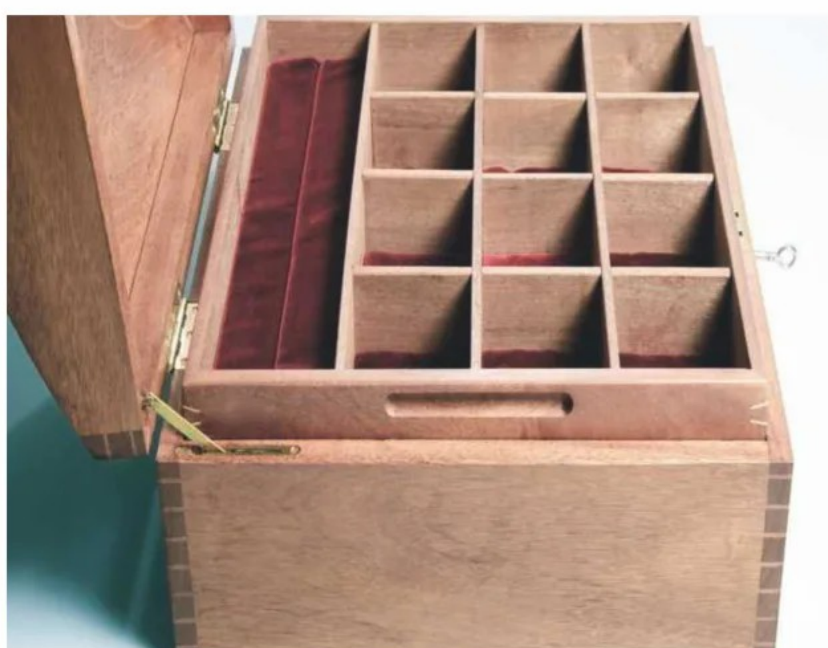
16 On this box, I've used conventional hinges with a separate sliding stay recessed into the side panel. The internal tray uses spline joints on its corners
