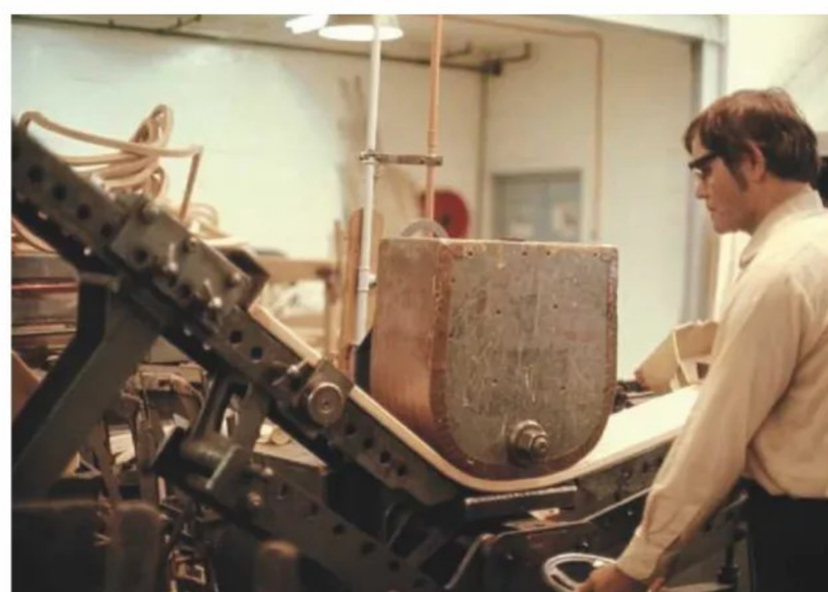
The operator turns the wheel, which moves the steamed parts up to the former. Other finished bent parts can be seen in the top left
