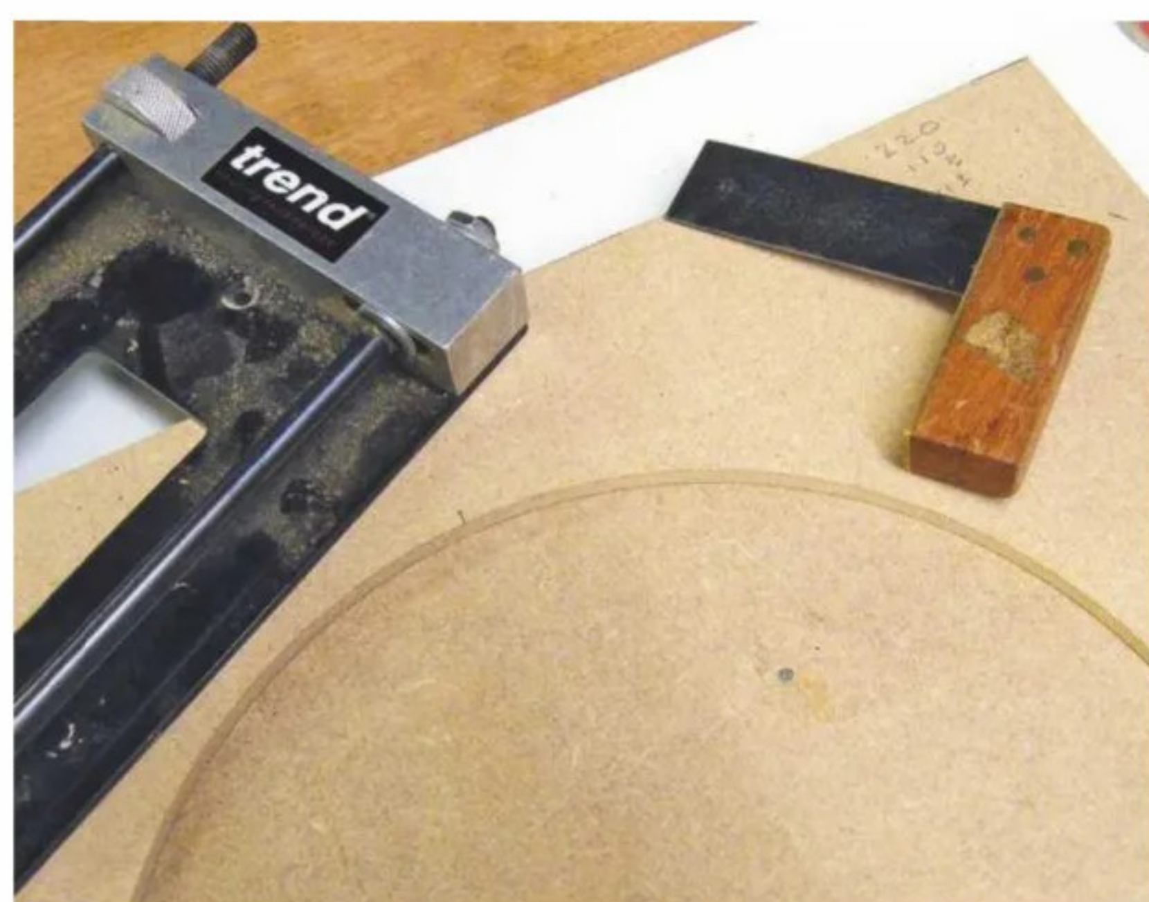
3 The second MDF circle needs to be a perfect fit into the first hole
