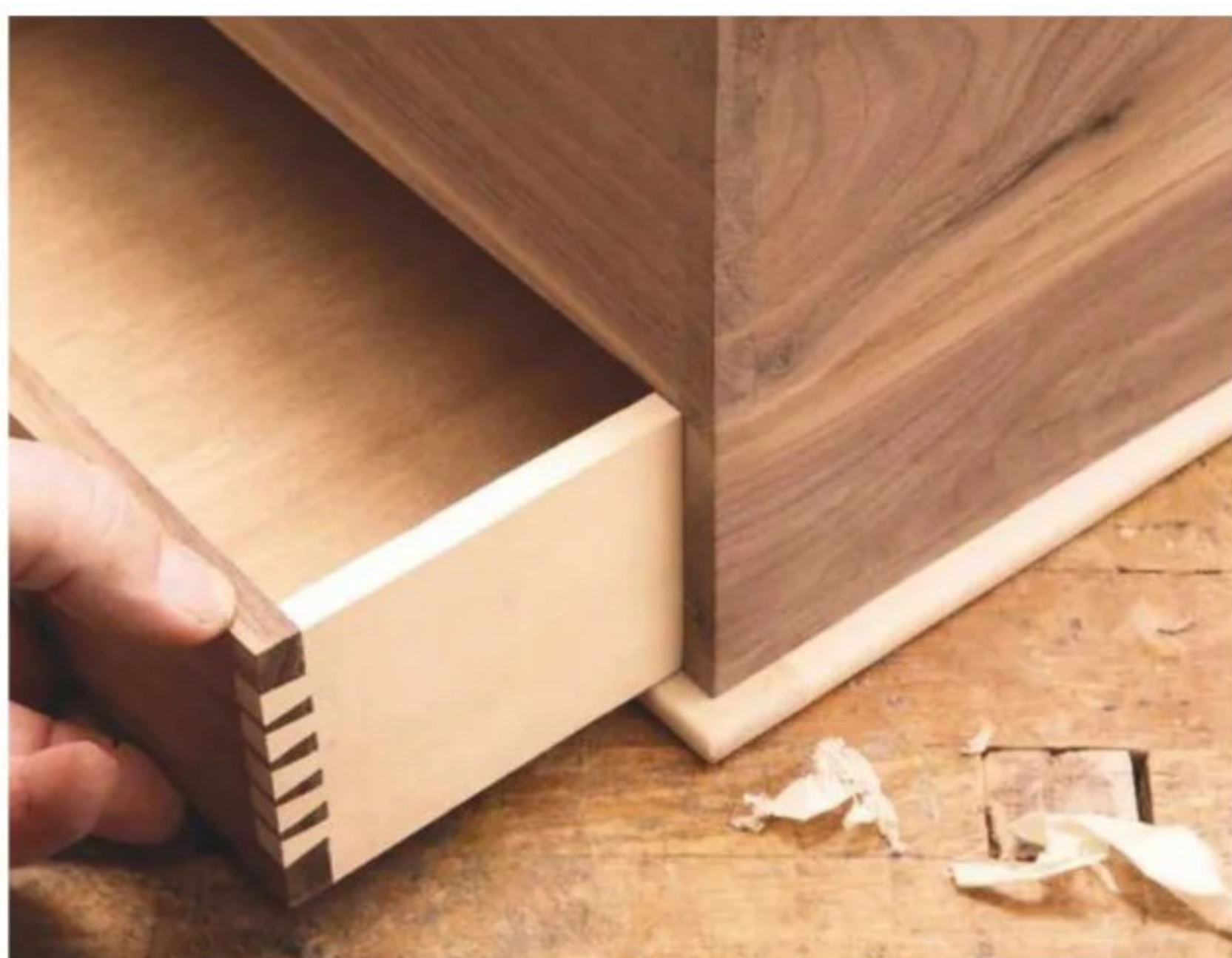
8 Drawers incorporated into a box need to slide smoothly without tightness or wobble
