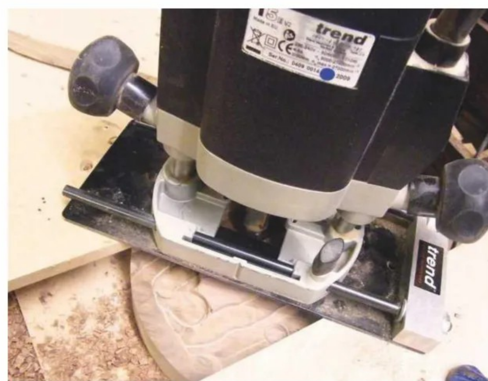
18 Repeat the process to leave a trench on the wheel's rear face
