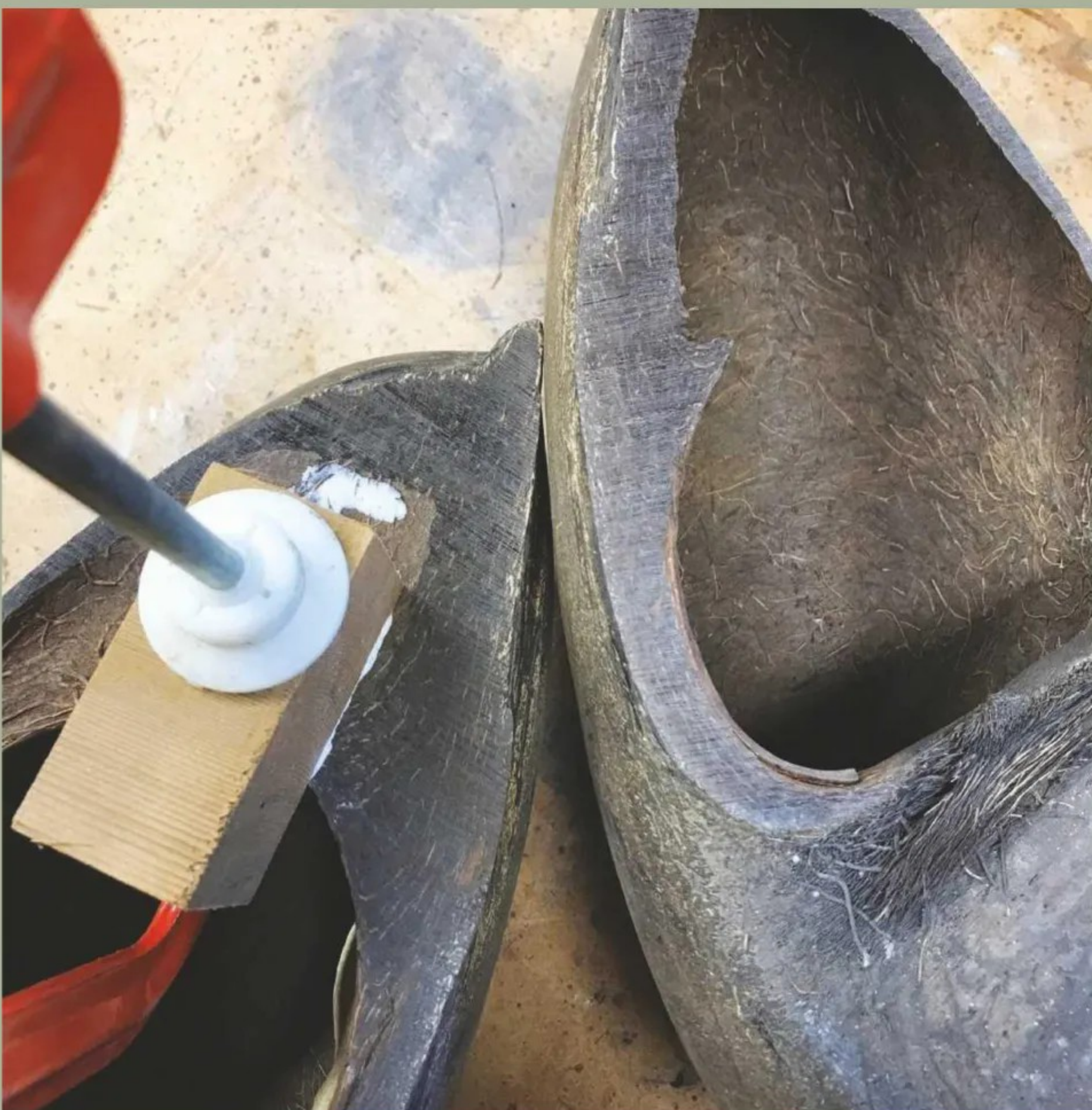
4 Thinking ahead, I decided to fix a wood block into the pod's centre so that, later on, I'd have something to drill into if I mounted it on a stand. I used a piece of western red cedar thinking this would be strong enough and easily bored. I then cleaned out and made good the cracks with a two-part resin filler
