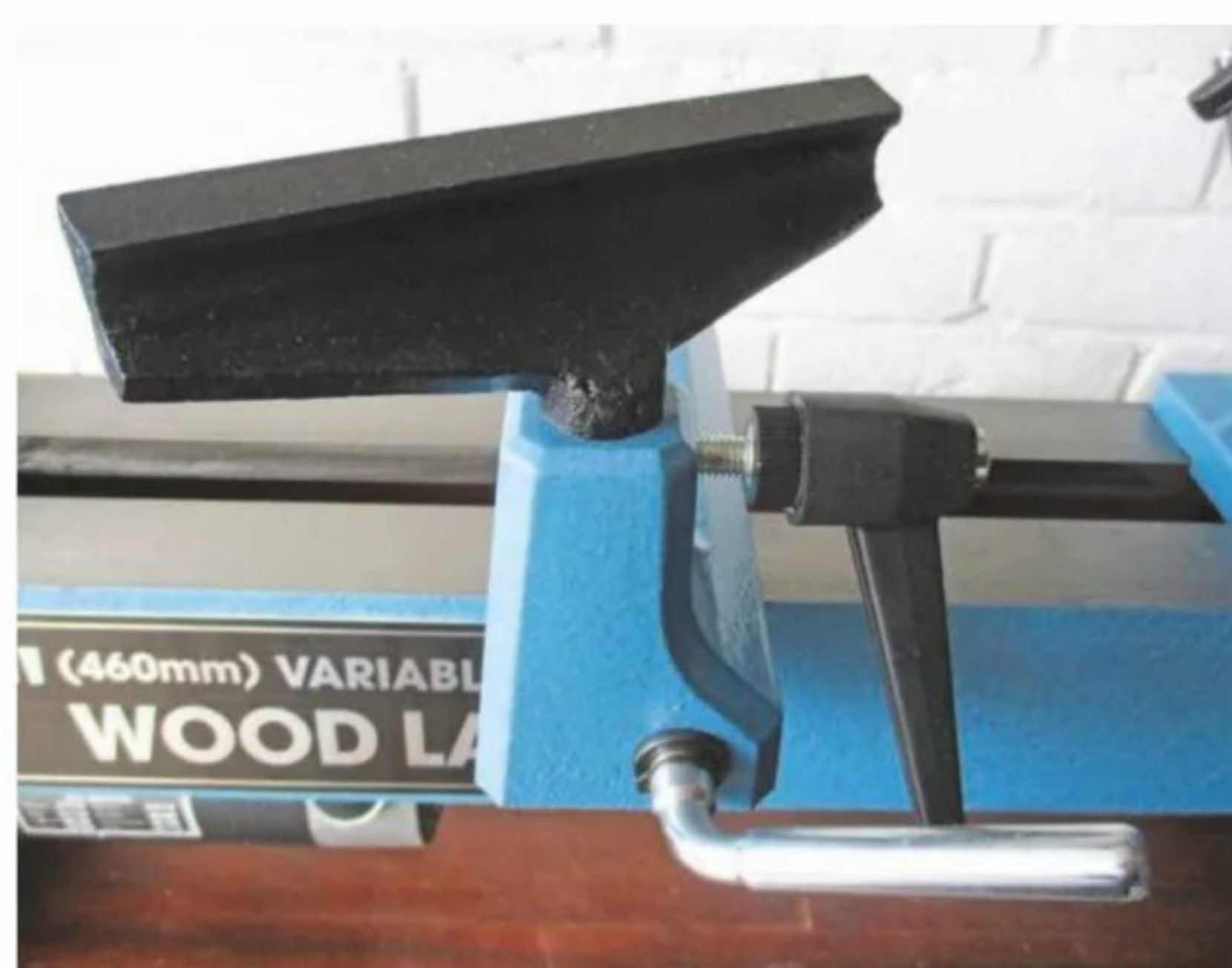
Cam lock to the bed; height locked with a screw
