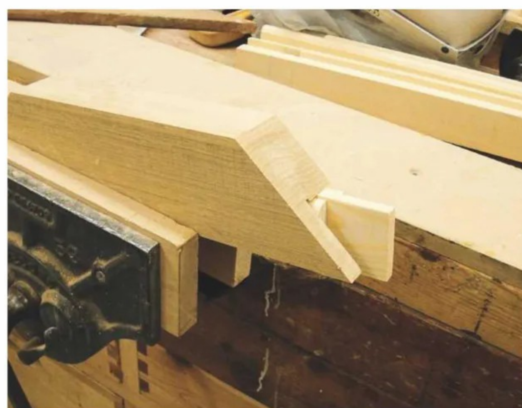
15 A simple mitre block is used to guide the chisel...
