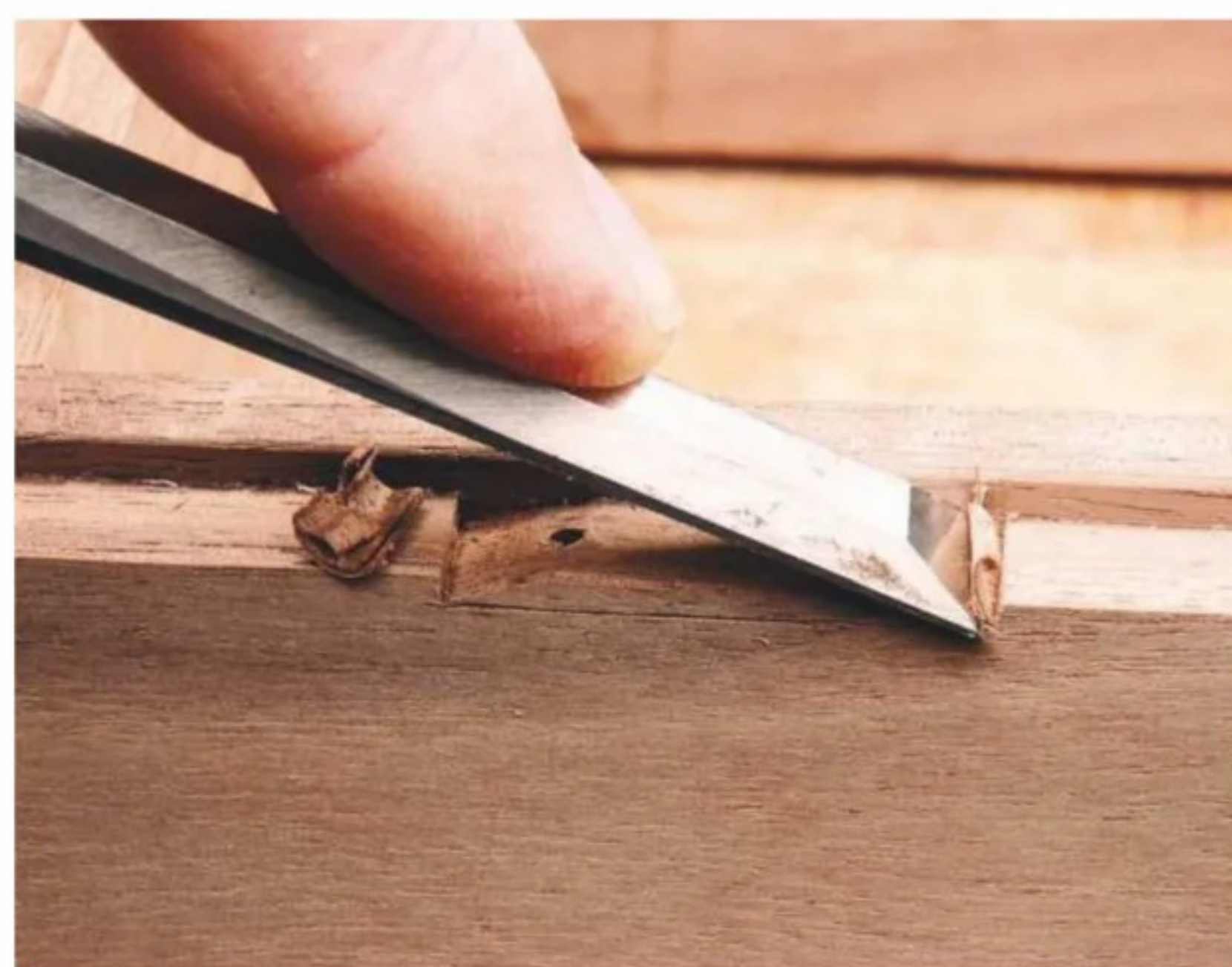
12 Before fitting a conventional hinge, I rebate a shallow mortise into a box's back edge
