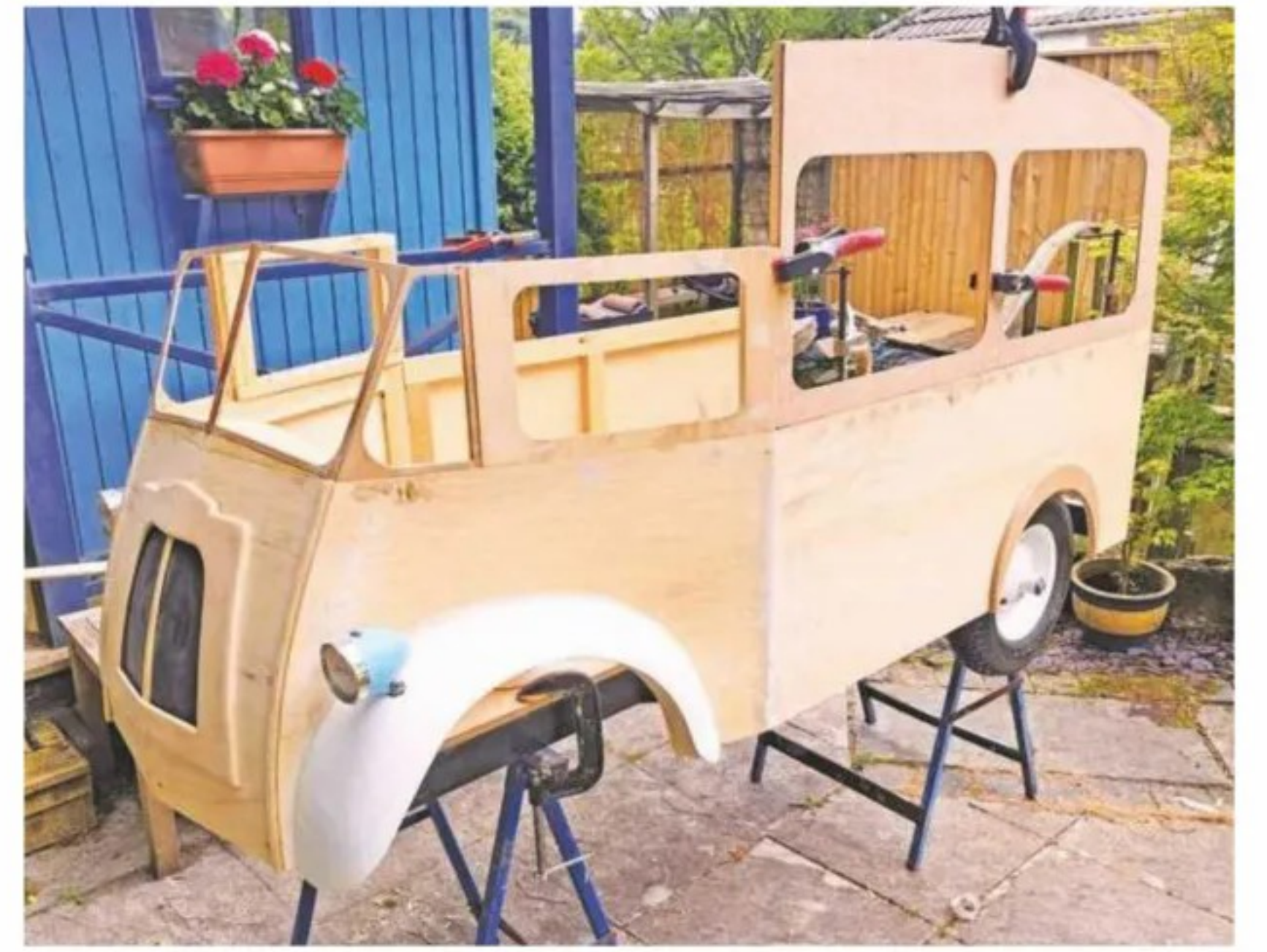
9 Windows were carefully cut with a jigsaw
