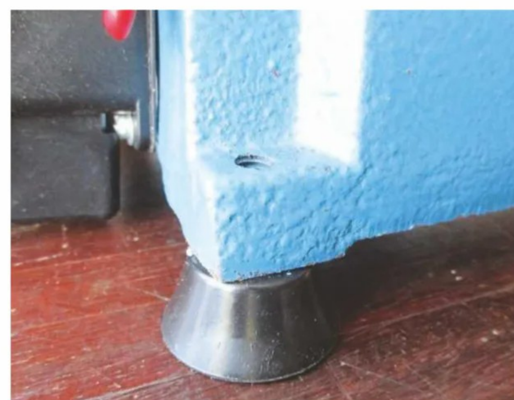
Rubber feet keep the lathe in place
