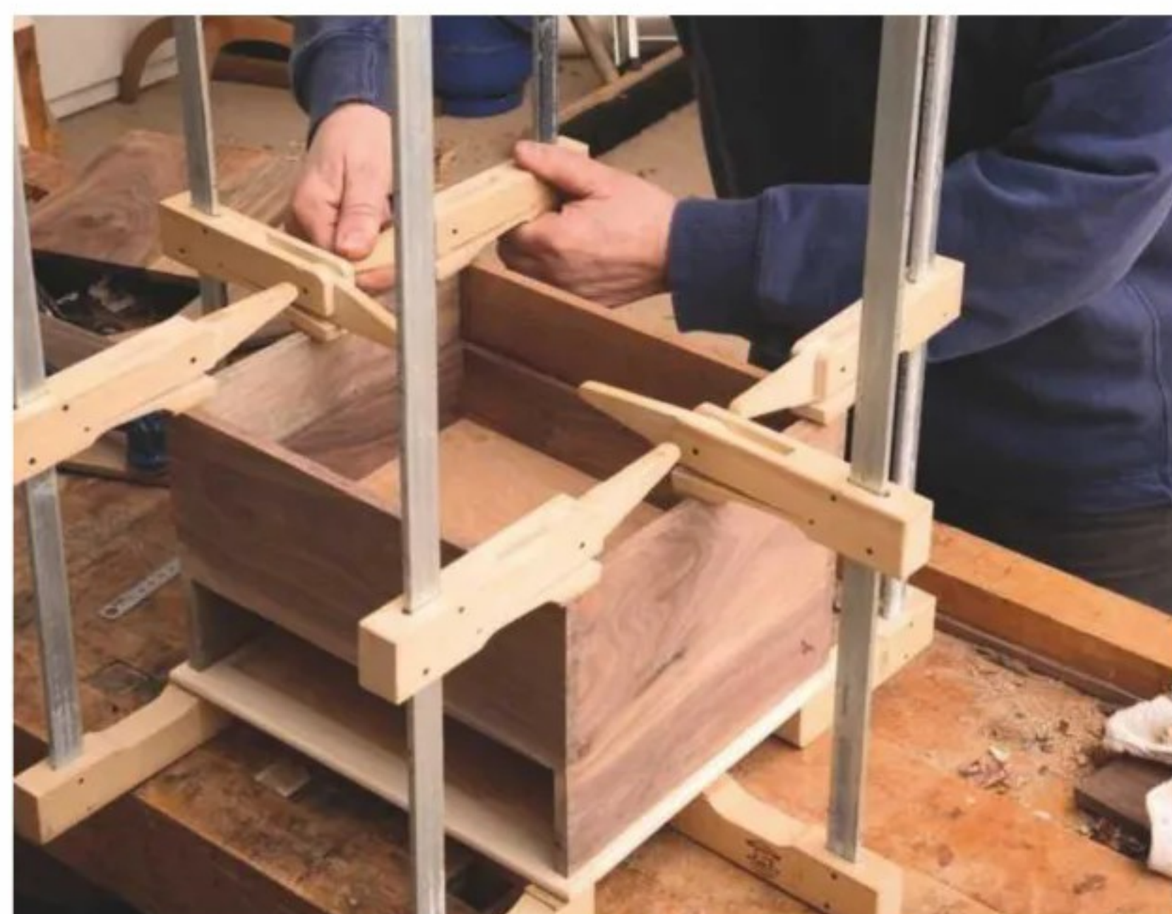
4 Once glue has been applied to the joints, they're pressed together using lightweight clamps, then left to set
