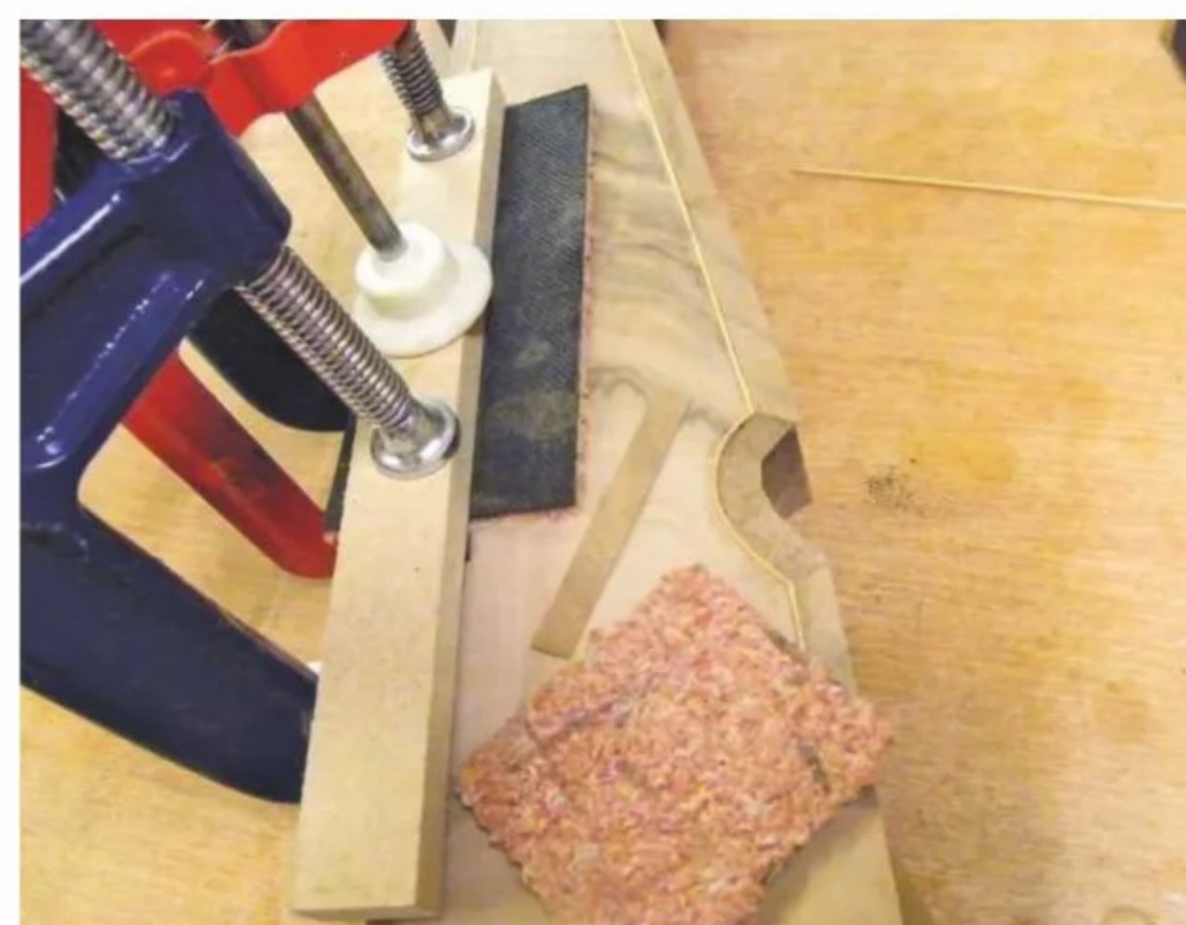
12 Add the cross-banding in stages, and cramp in place using a carpet tile offcut
