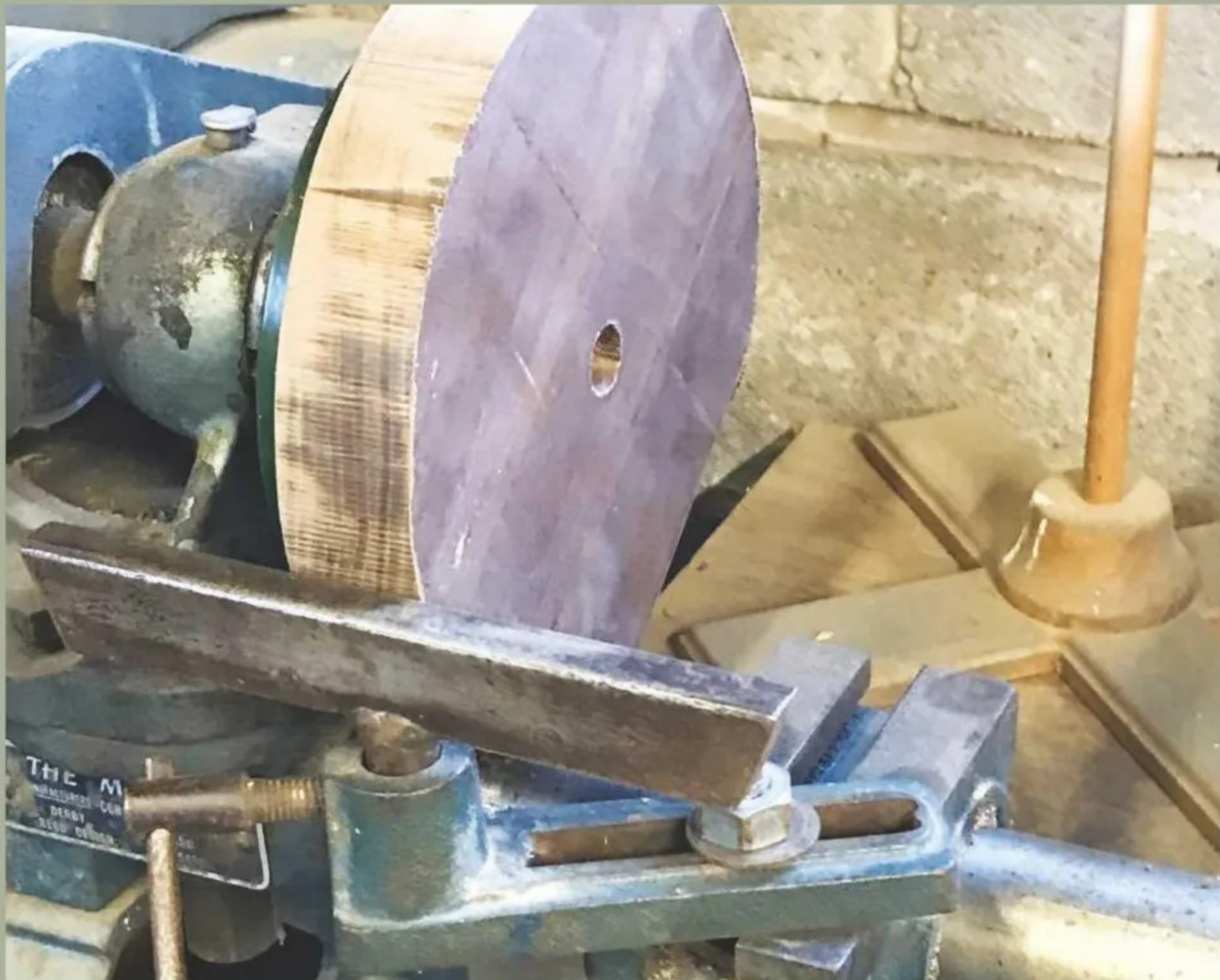
13 I didn't want the base disc to be too fancy and detract any interest away from the pod, so I simply turned an ovolo edge onto it. Once cleaned up and finely sanded, I coated the show wood surface with some lacquer
