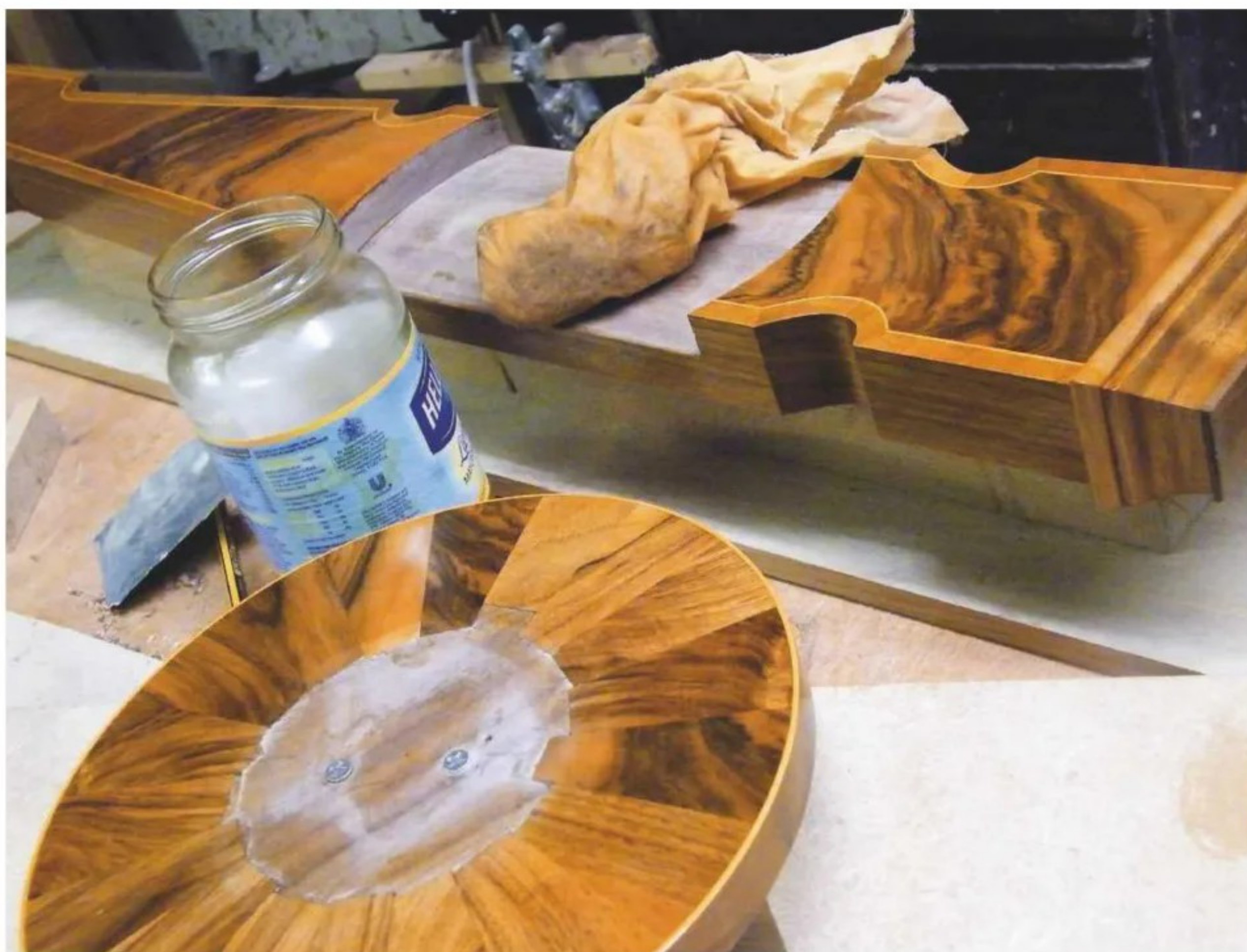
24 Polish, wax and assemble the parts and glue them together, ready for the instruments
