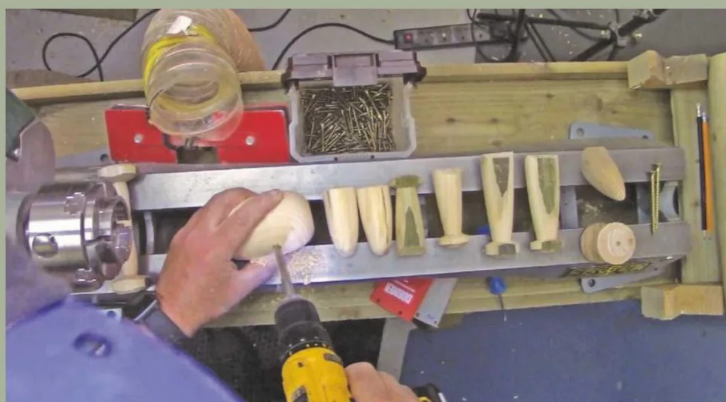
26 I then followed it through with a 5mm hole and drilled through the neck
