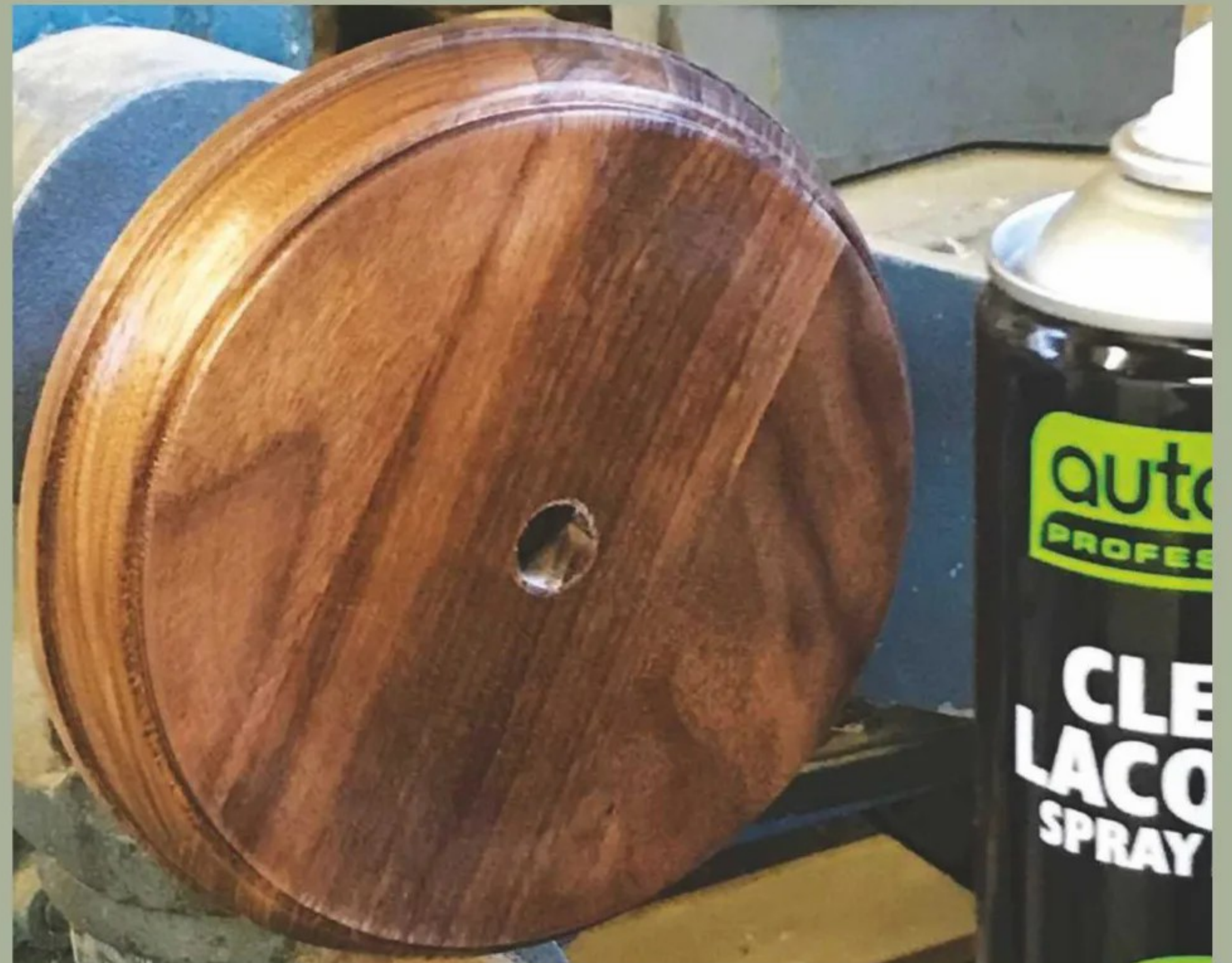
14 This was cut back with fine steel wool on the lathe, then waxed and buffed up with more Fiddes Rugger Brown
