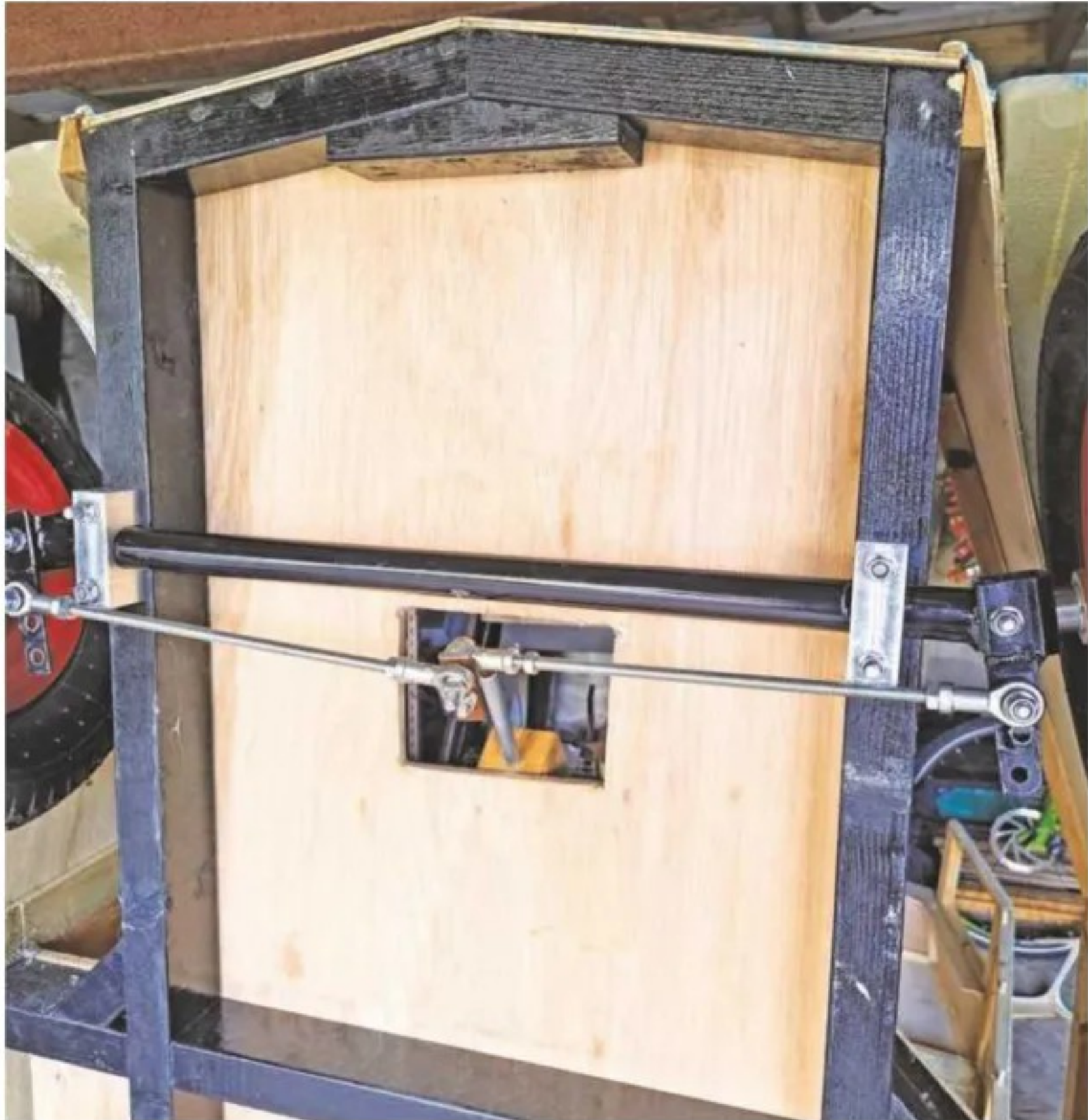
16 The steering follows that of traditional pedal car/soapbox design
