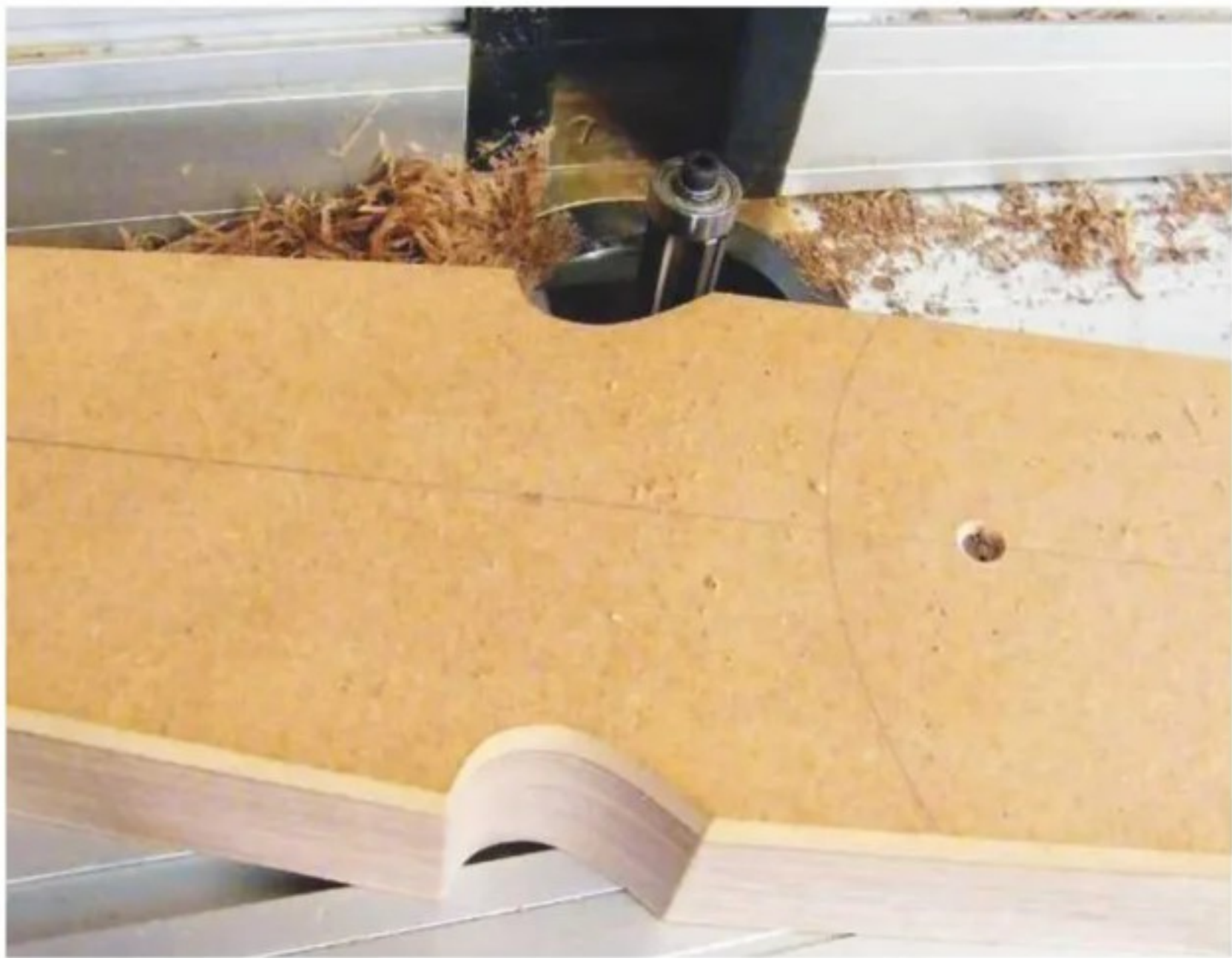
7 Extra blades give a fine finish as the cutter follows the template round the column
