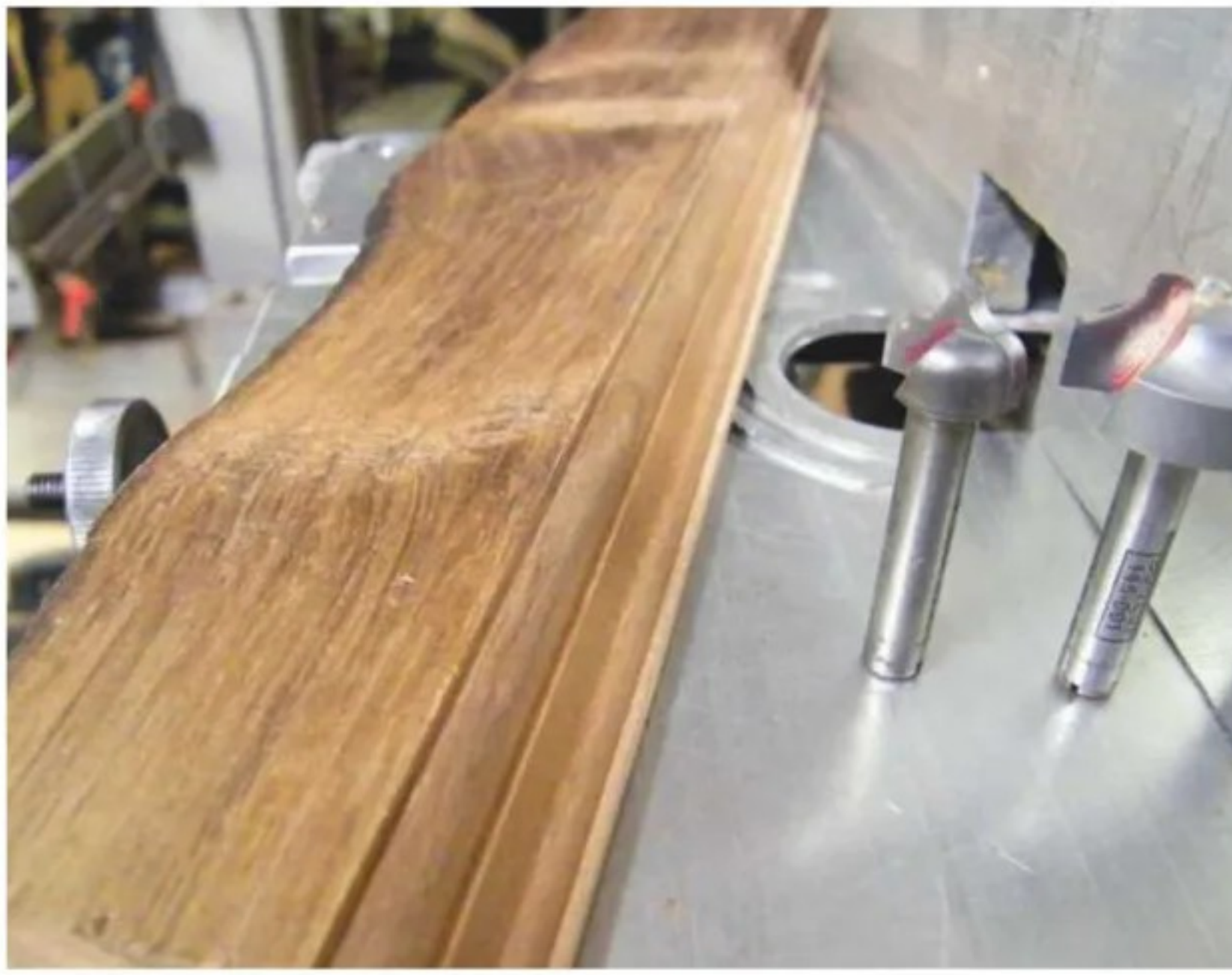
20 Mould the edge of a wider strip, then trim off the width required...
