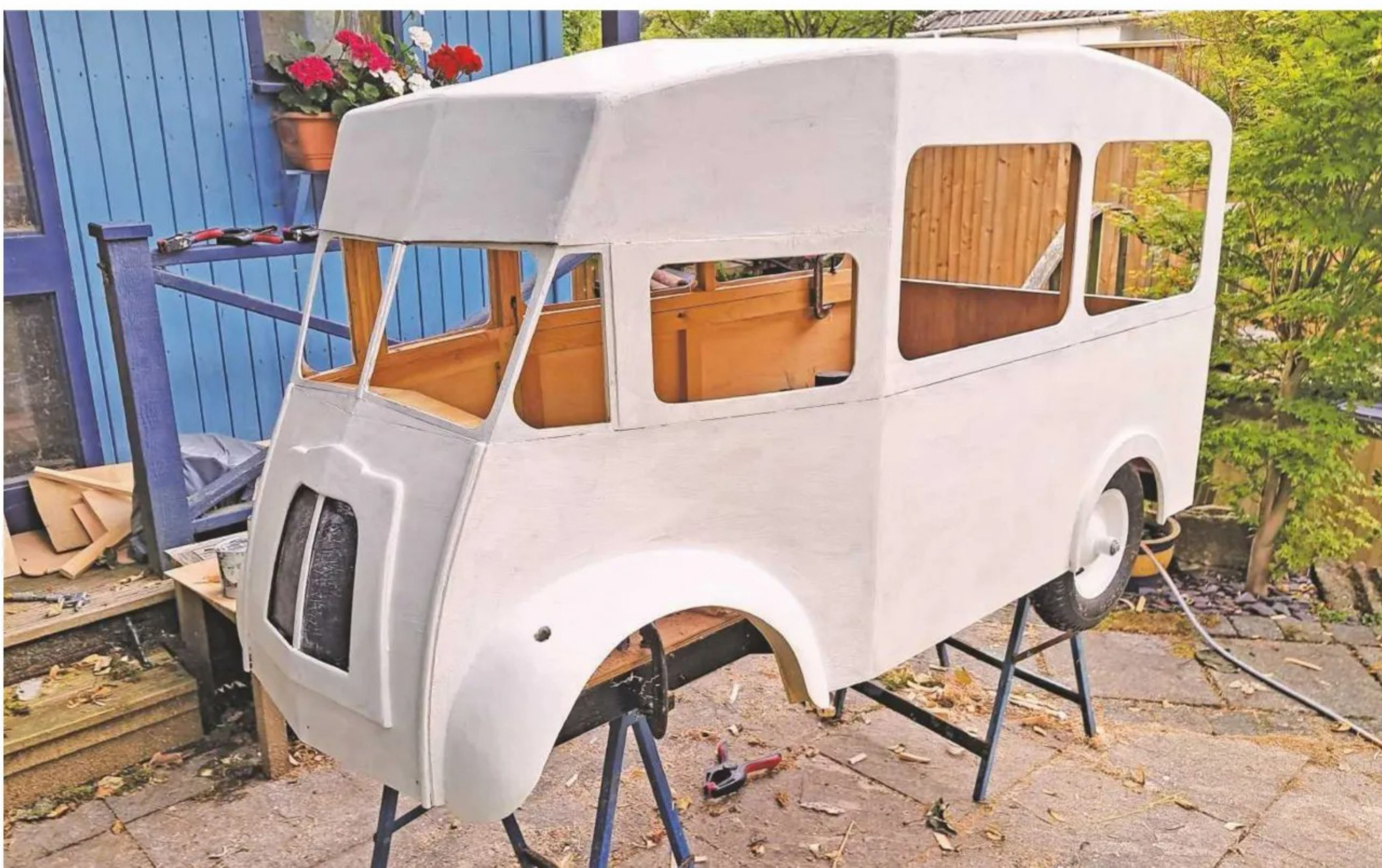
12 Applying coats of acrylic white primer prior to sanding down
