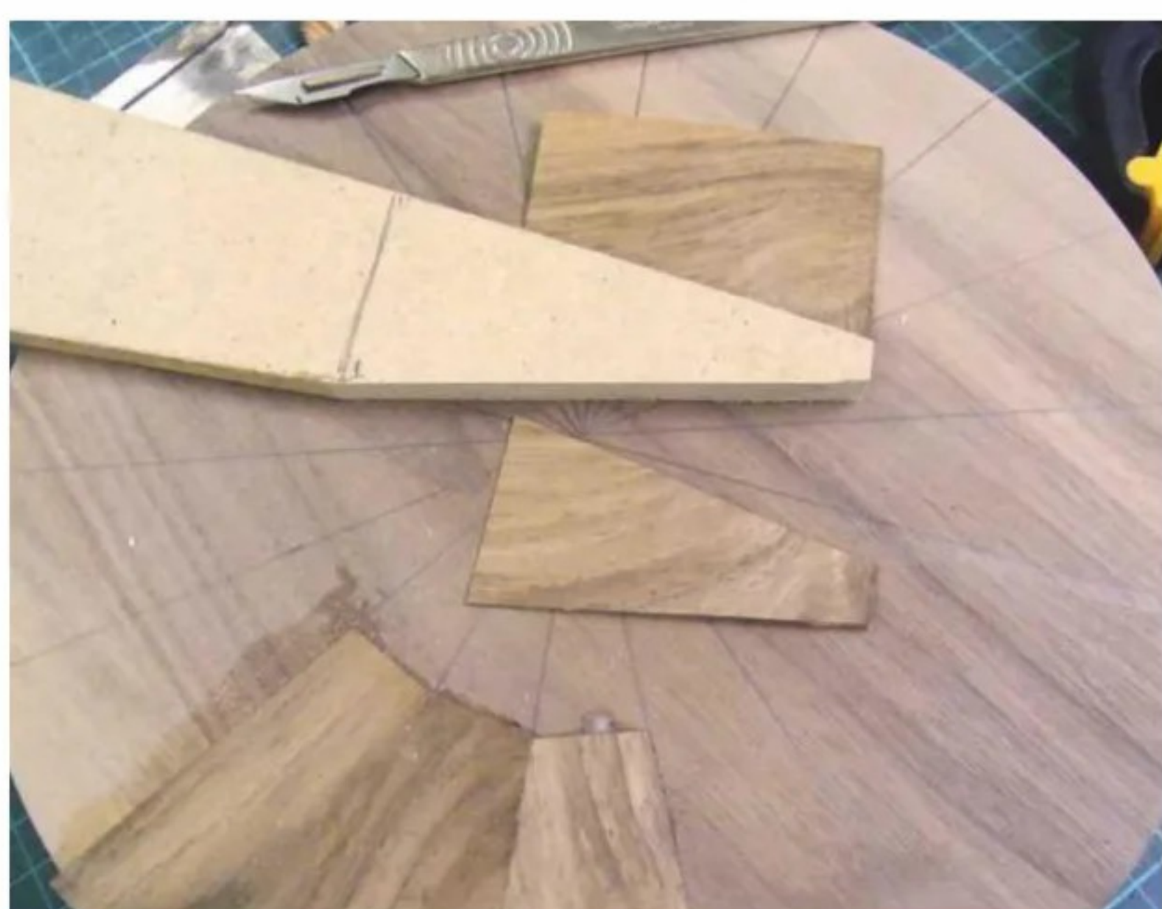
13 Divide the wheel into 30° equal segments and glue on the veneer wedges
