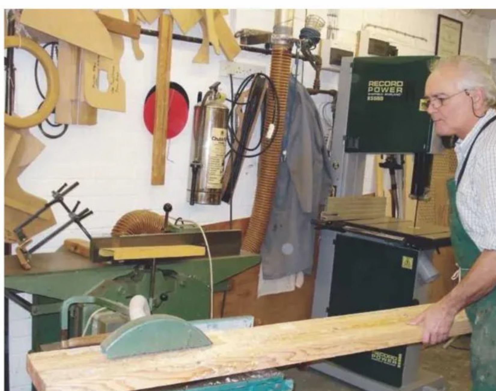
1 I ripped down a 225mm-wide board to make two 100 × 50mm sections for the stiles
