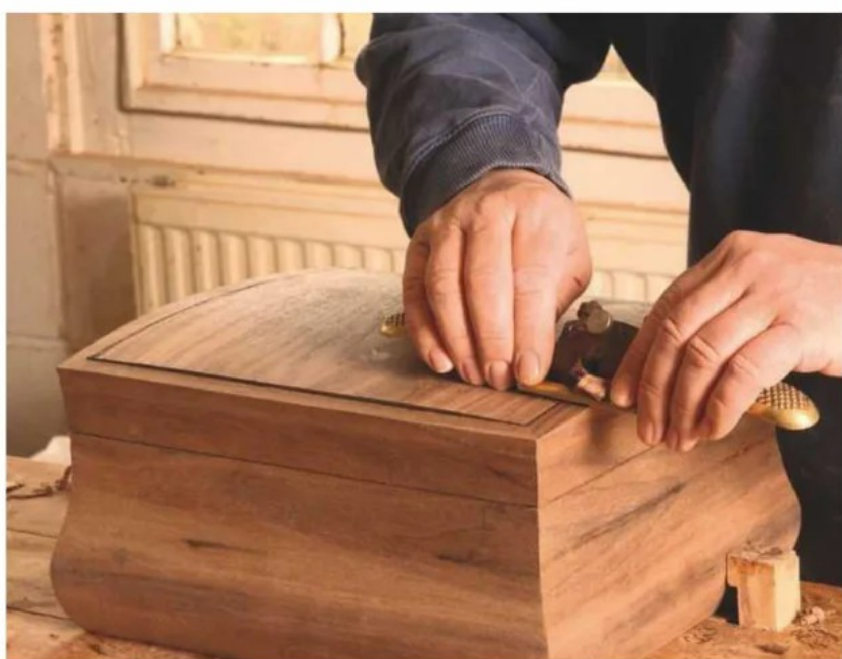
7 Using a spokeshave to shape the sides so that they match the box's curved lid
