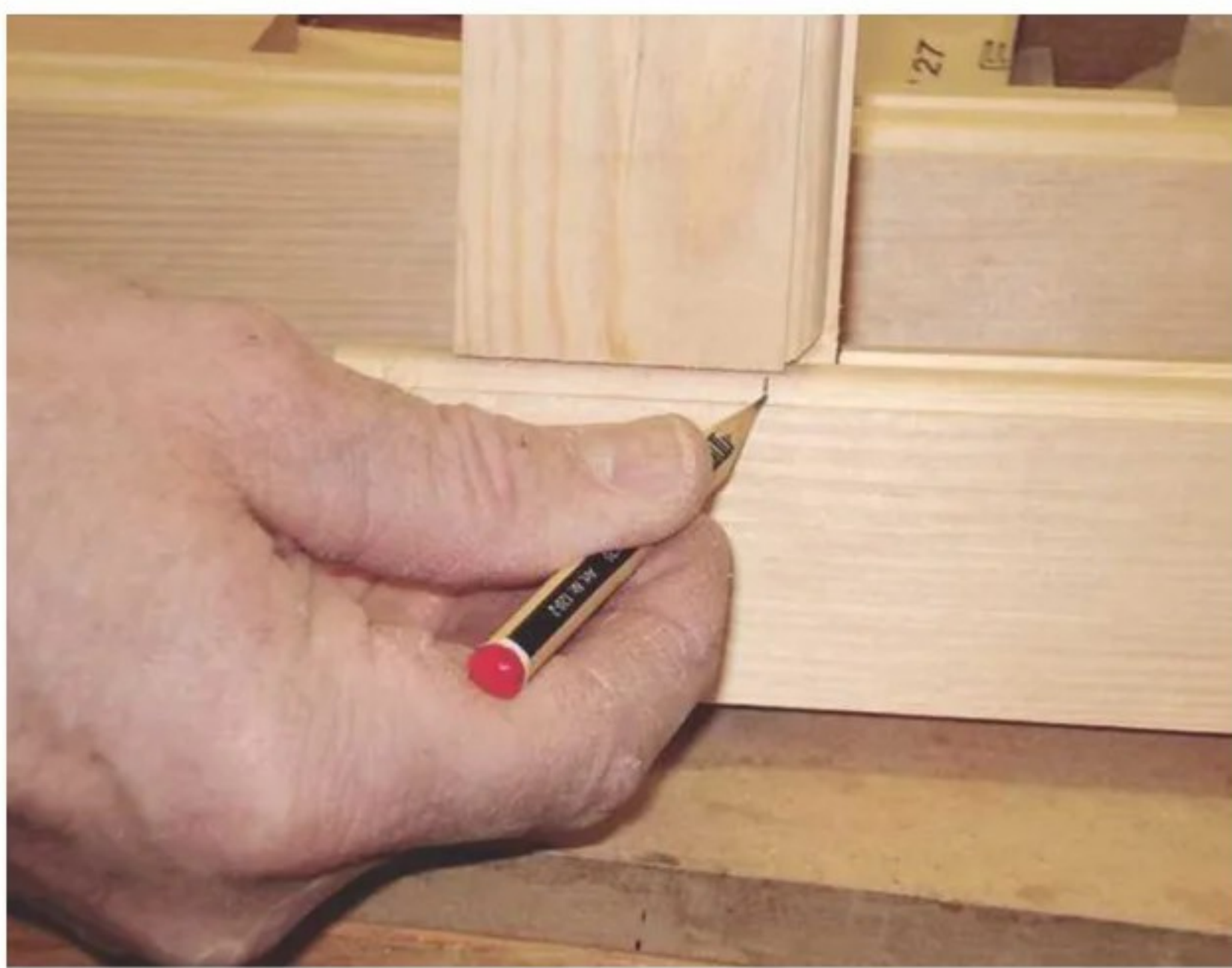
19 Rails are offered up to the stiles, which are marked...
