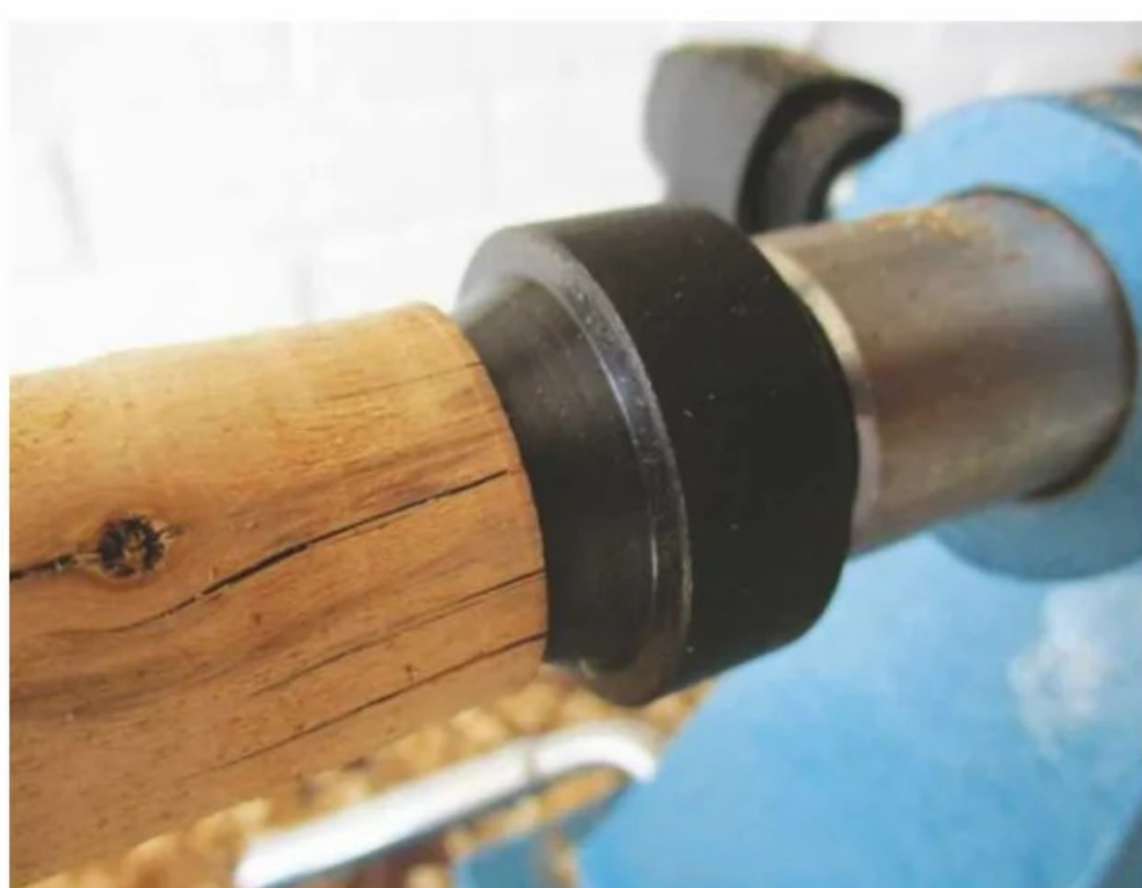
Cup centre holds end tightly
