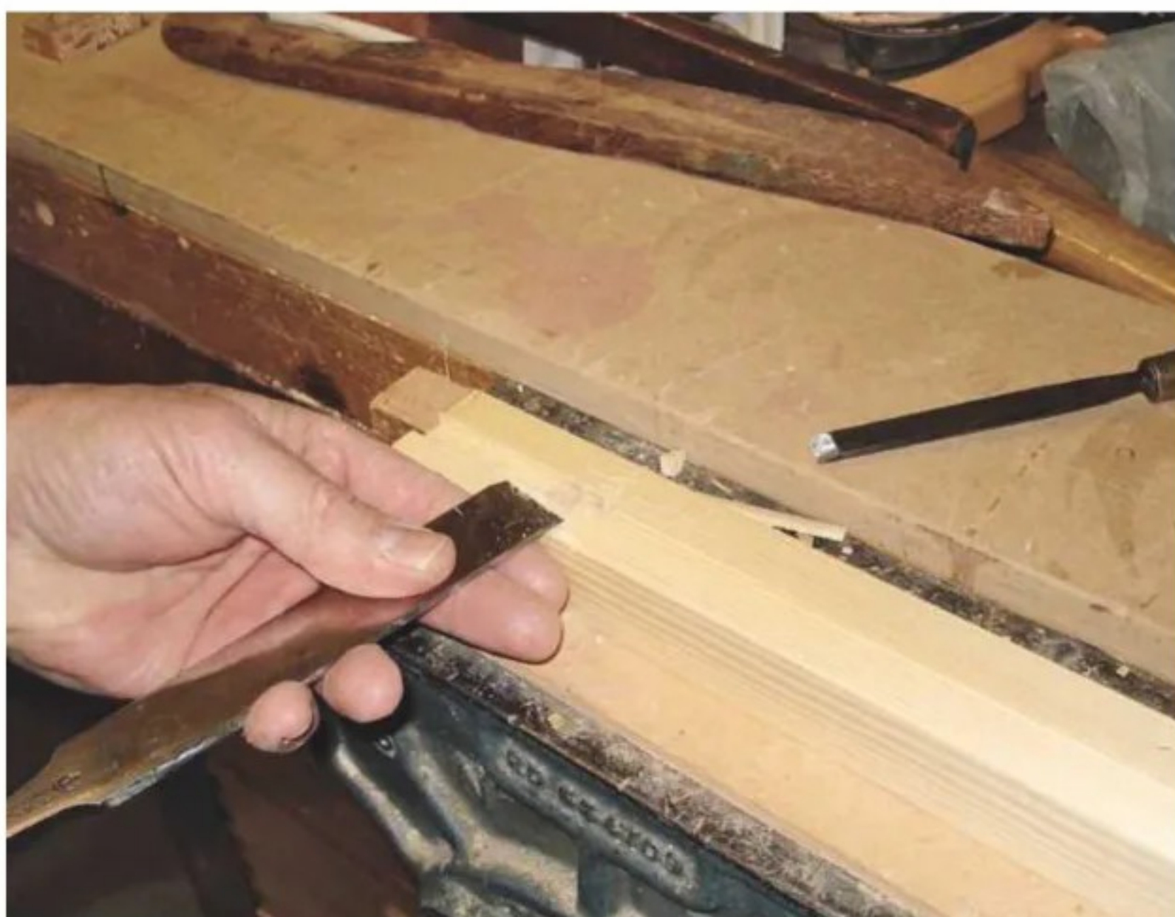
21 ... a flat area ready to receive the rail's square shoulder
