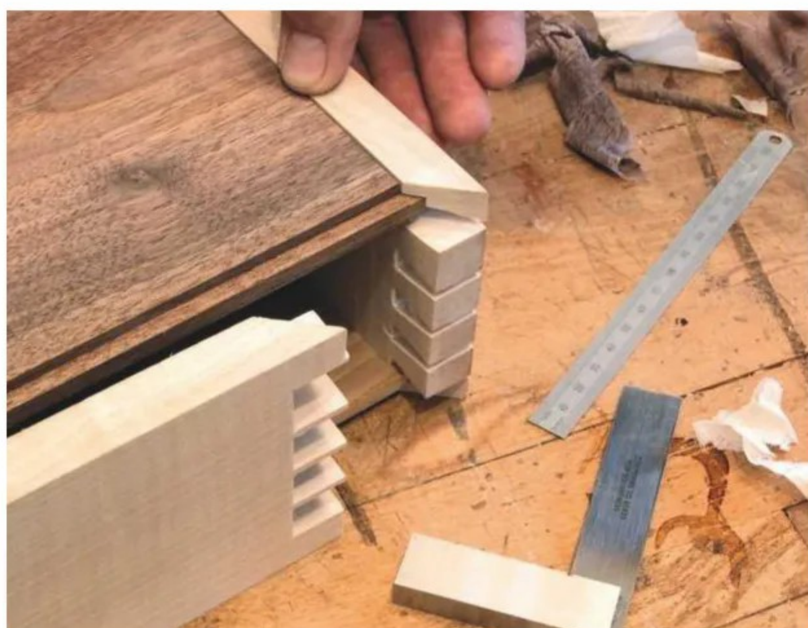
3 Here I used mitred dovetailed corners and when assembled, the box's top and bottom panels are trapped in grooves within the sides
