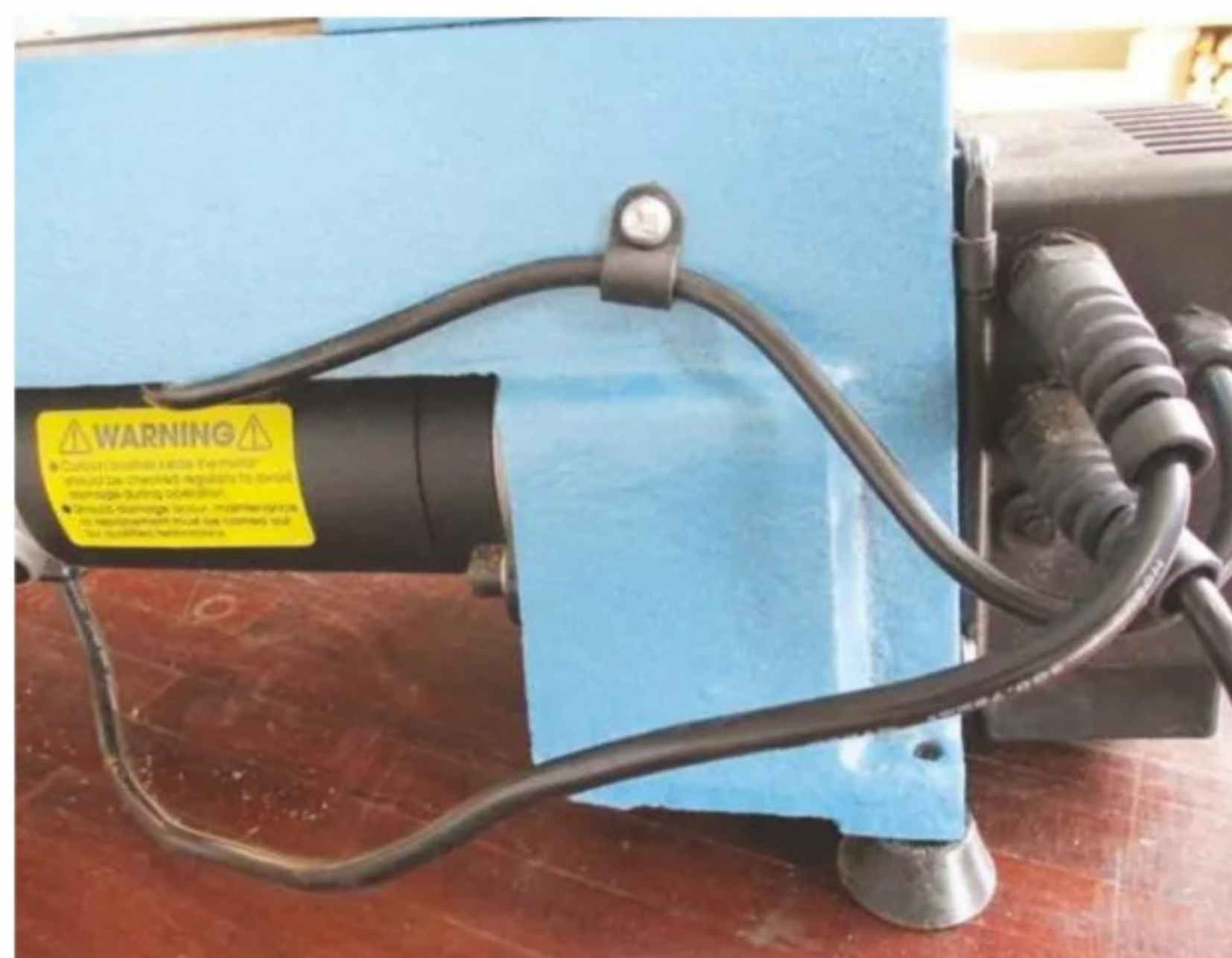
One cable clip, two cables
