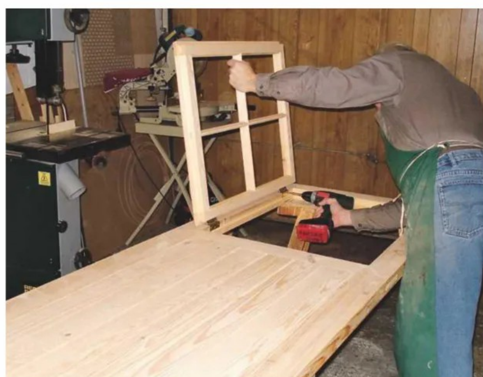
25 Fitting the light to the door – aren't cordless drills brilliant?
