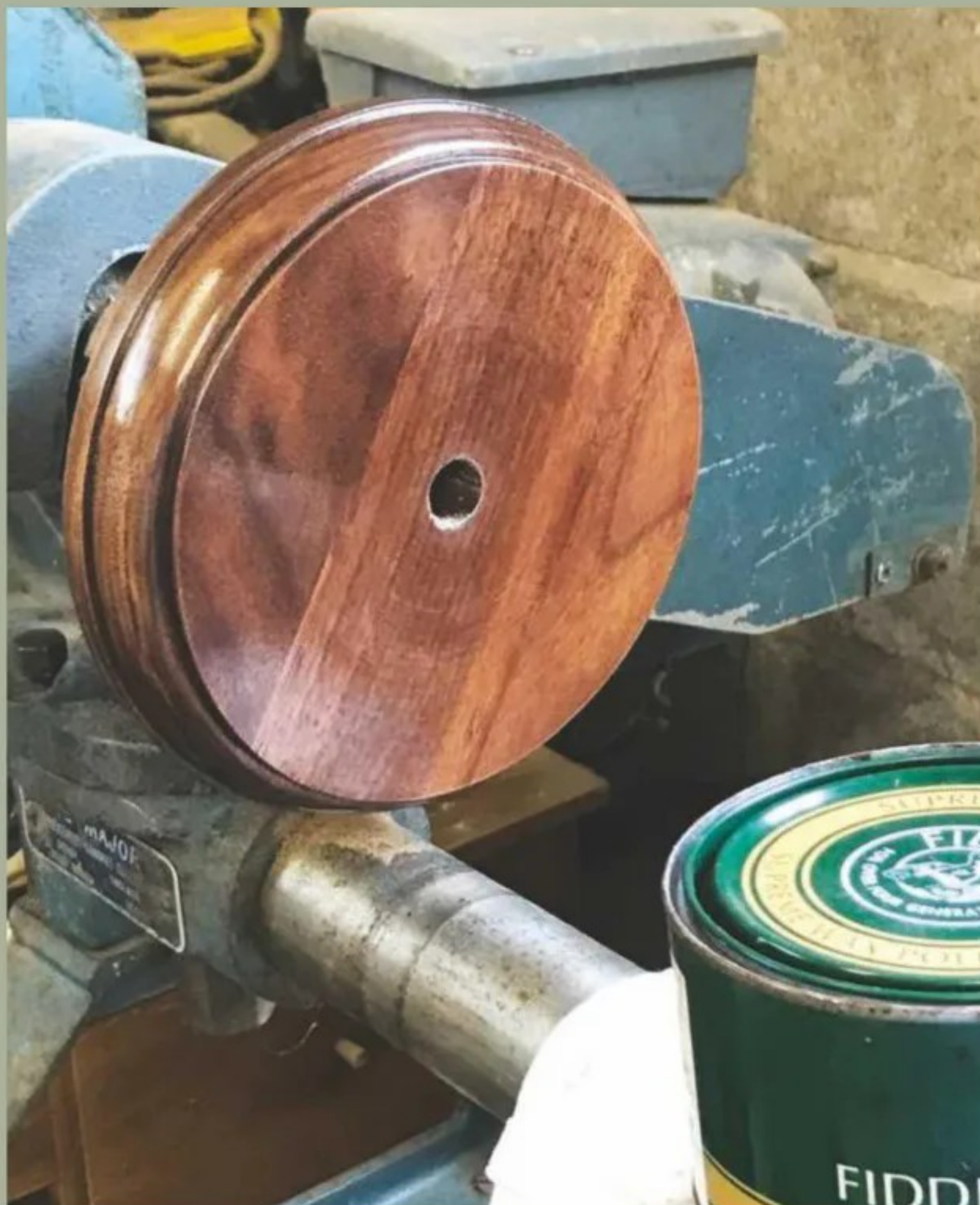
15 The fixing screw holes on the disc's bottom needed to be level and the display rod fixed in place. By this time, I'd cut the top of the rod into a chisel shape so that it'd bite into that internal block. I wanted the stand to be removable so that the pod could be easily transported
