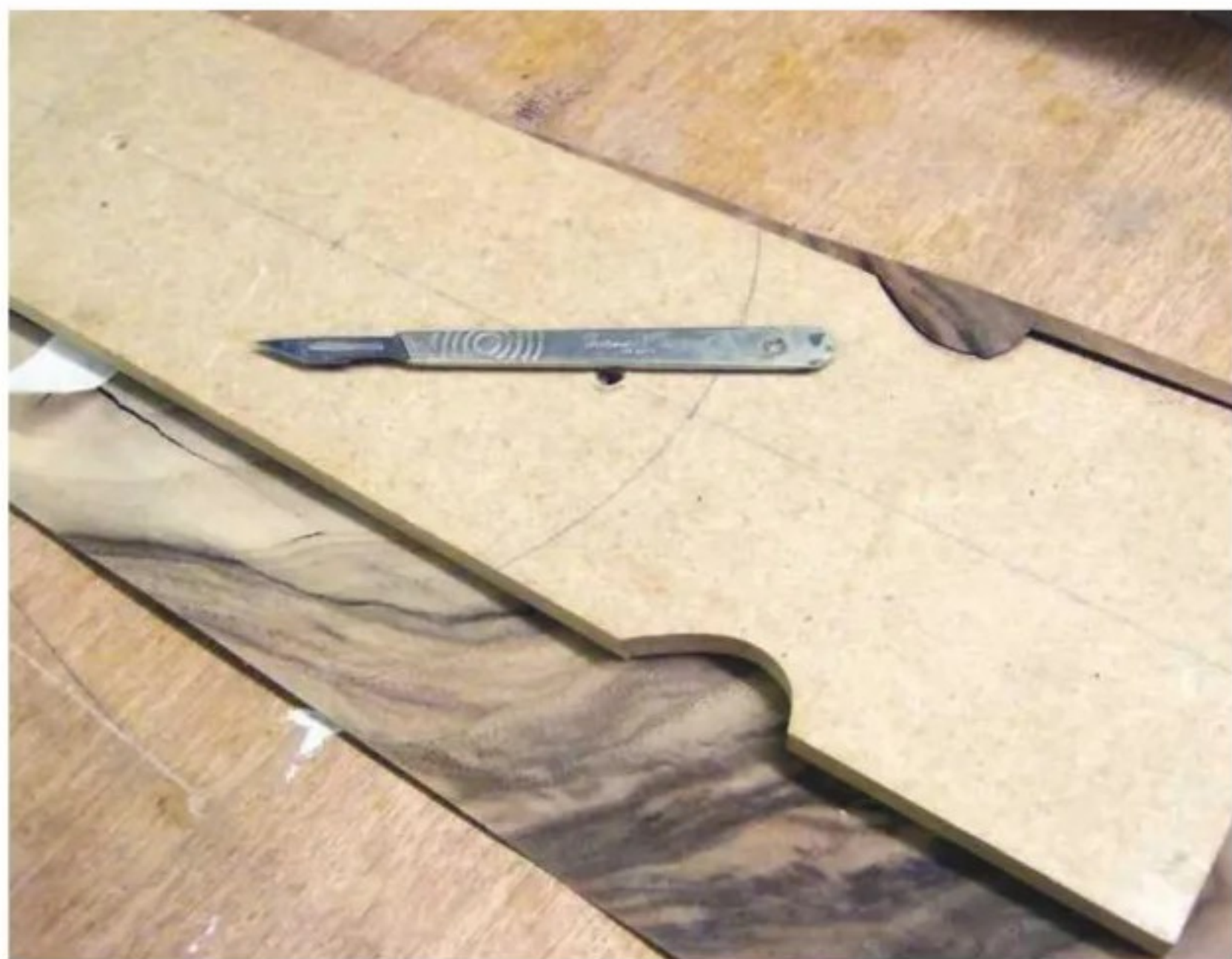
8 Use the template as a guide for trimming the figured walnut veneer
