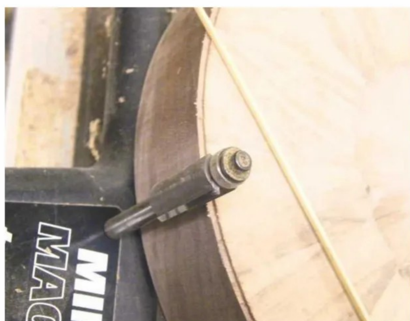
14 Note the reduced bearing on the trimmer for cutting the stringing rebate
