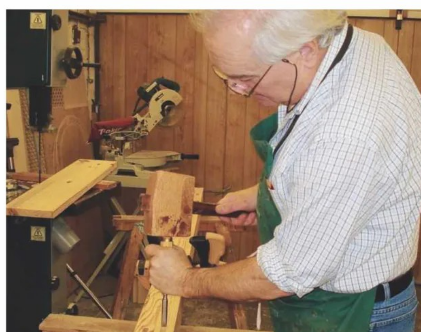
4 ... to cut the wedge from the mortises' outsides by hand
