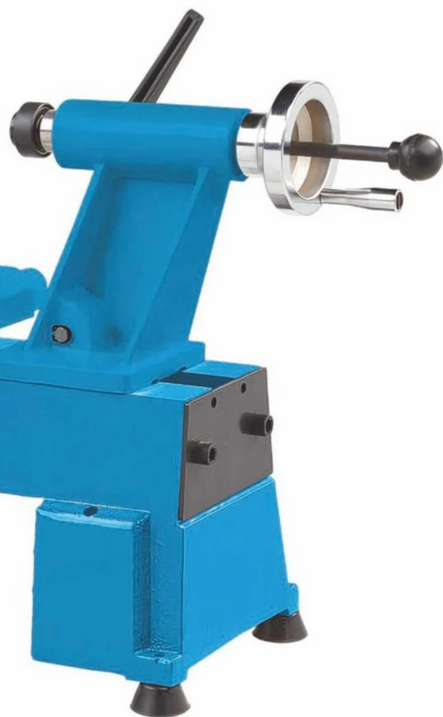
Controls swing out of the way for belt access
