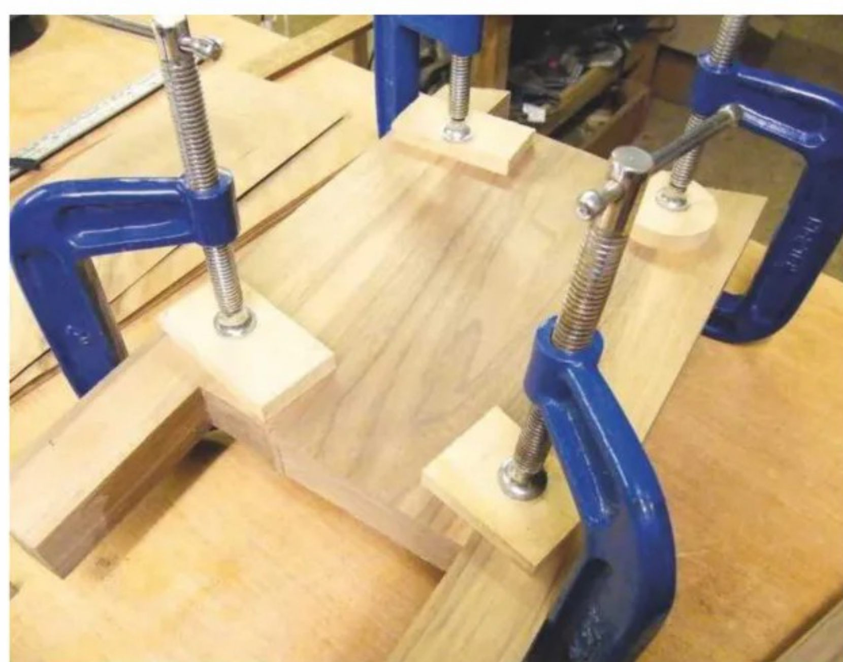
5 Glue pieces of walnut together to make up the wheel's width
