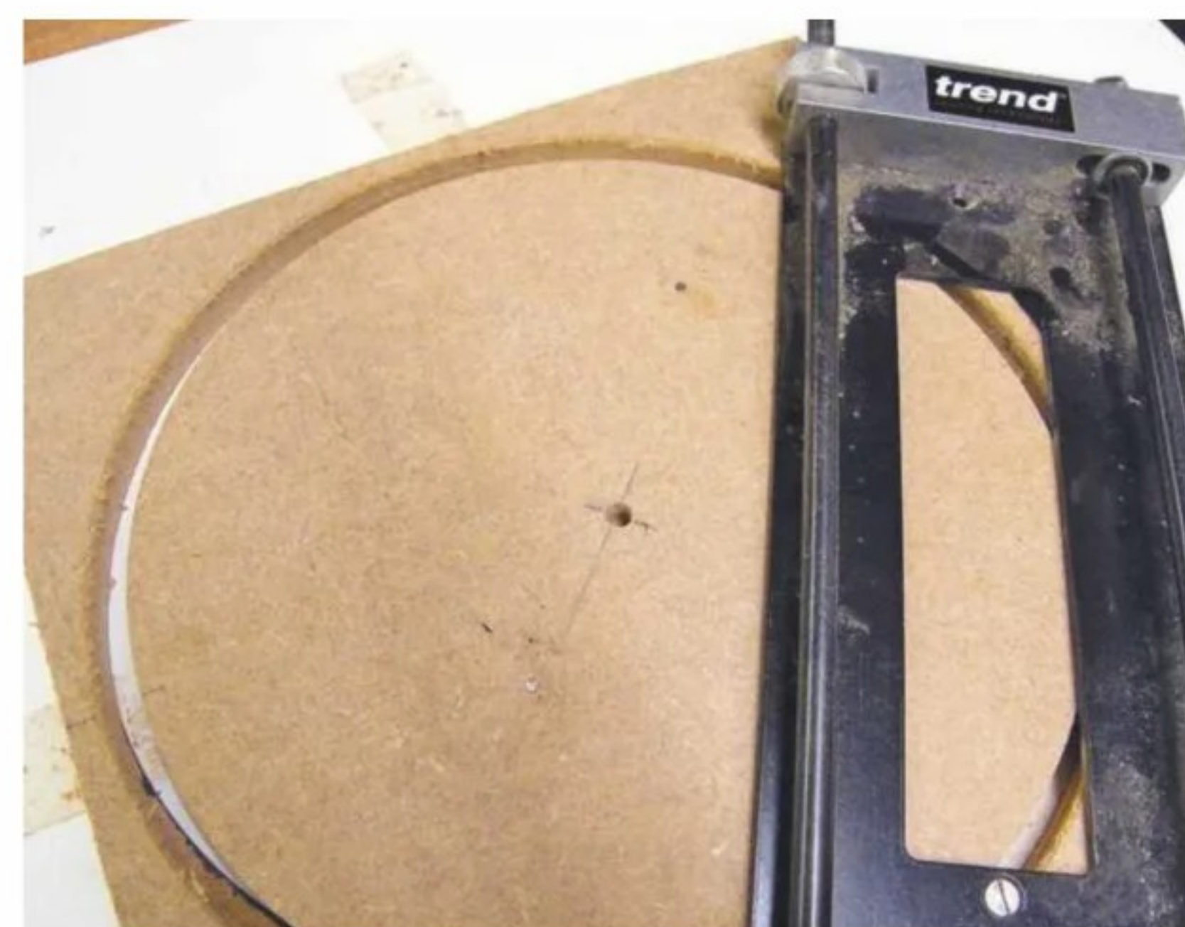
2 Use the jig to cut the MDF template for the barometer's wheel part
