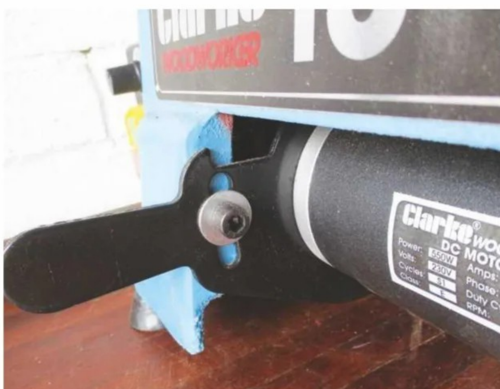
... but don't forget to release the motor first
