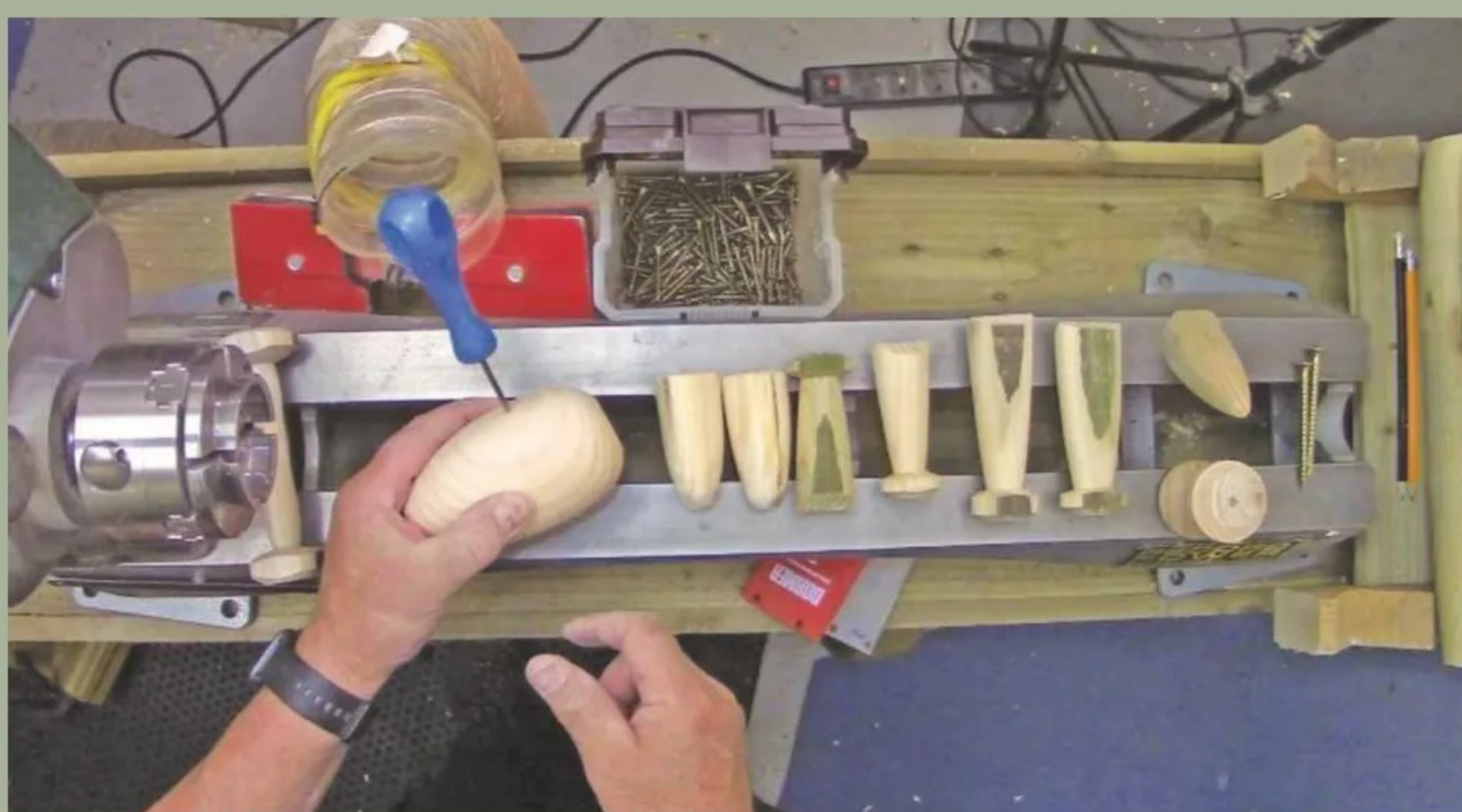
25 Now that the turning and sanding were completed, I drilled a 10mm hole to half the head's depth, starting this off with a gimlet or bradawl
