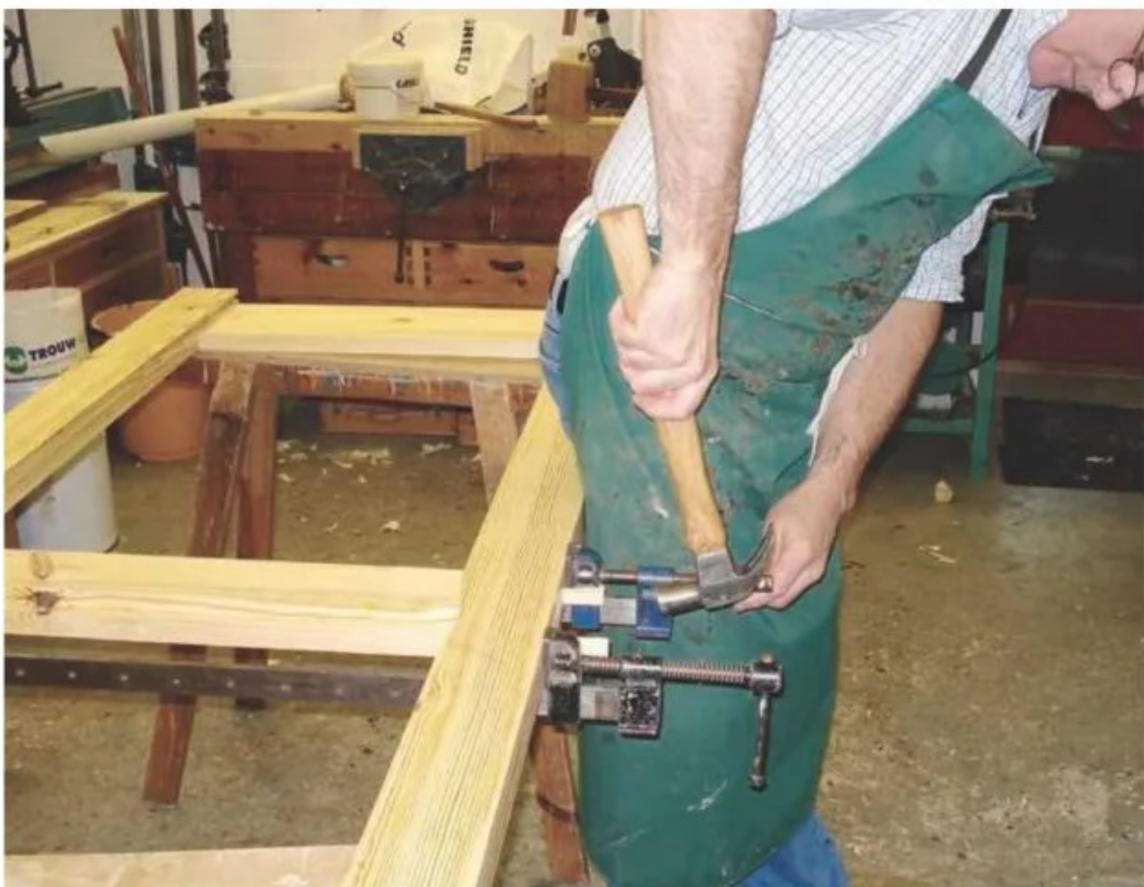
9 The frame is now glued up, assembled, and the wedges driven home
