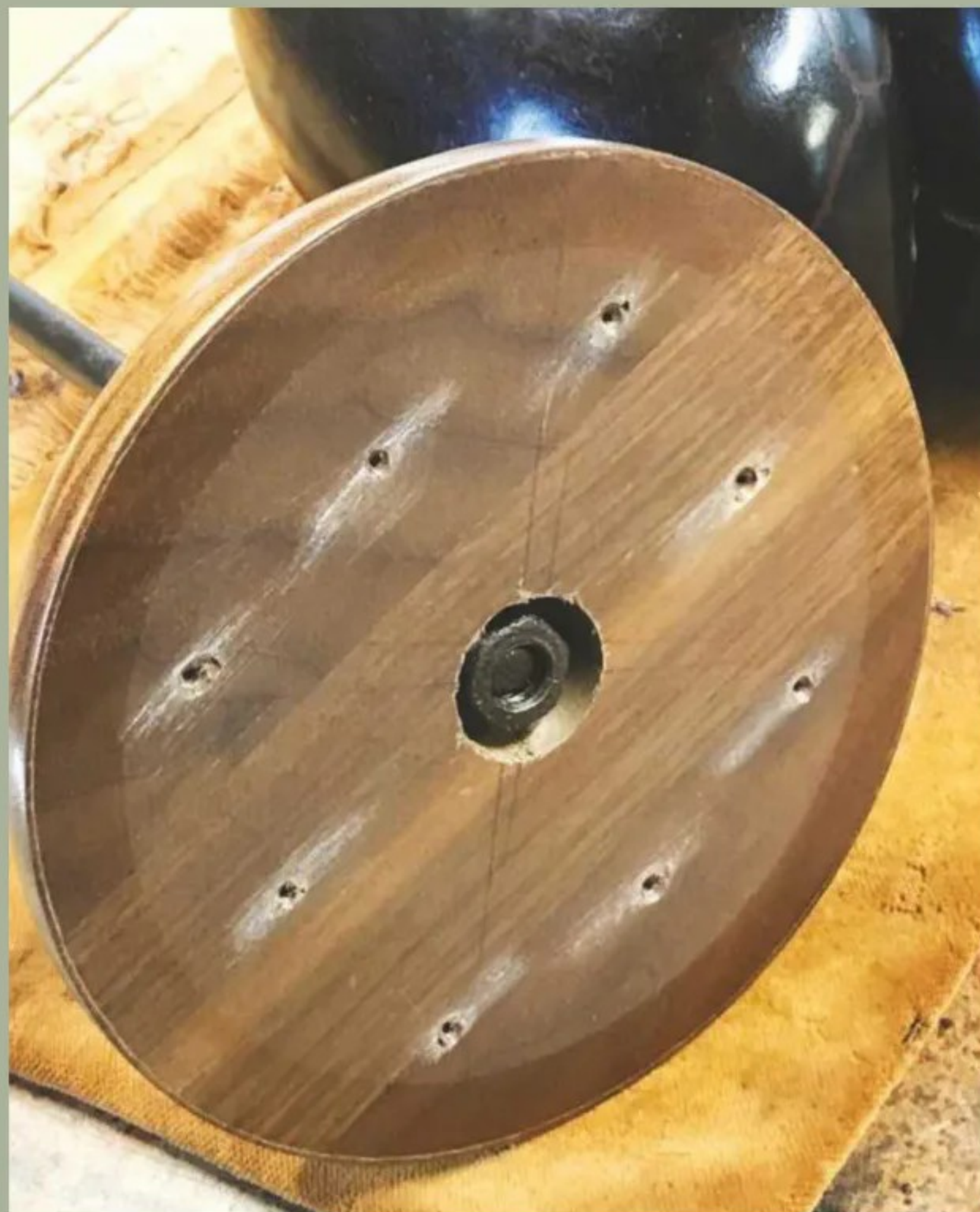
16 & 17 I have some very long wood-boring bits, and used a 14mm one to drill up into the pod from what's perceived as the lower end. I just managed to locate the block as well, so that was a good result. I put a rubber grommet on the rod's shaft to buffer the pod's bottom, stuck a disc of green baize on the underside and the job was done. The pod now sits on a sideboard in our lounge and is a talking point when visitors see it for the first time: a nice, natural sculpture
