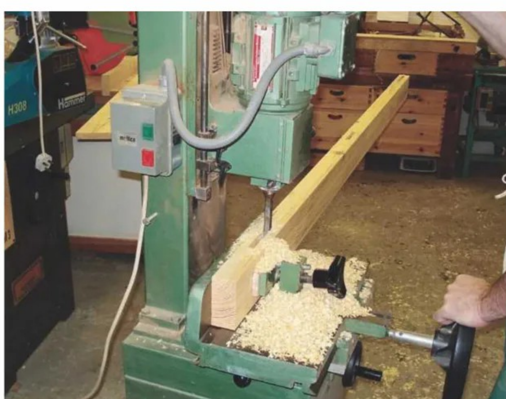
3 .. which I cut on the mortiser using a 12mm chisel, saving my chisel and mallet...
