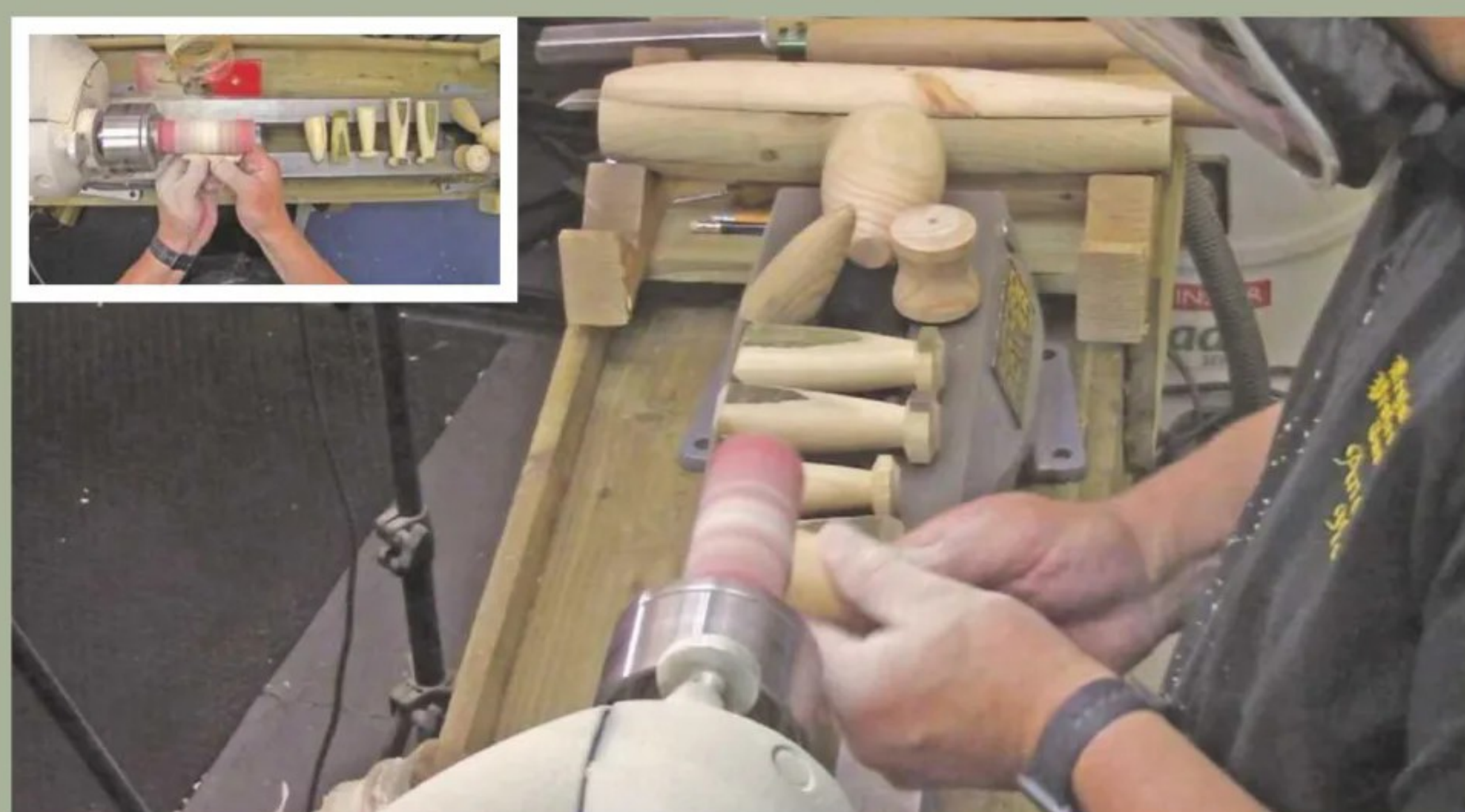
24 Finally, I sanded the offcentre turned ears using a Simon Hope cylinder sanding arbor, which created a curve on the ear interior and bottom
