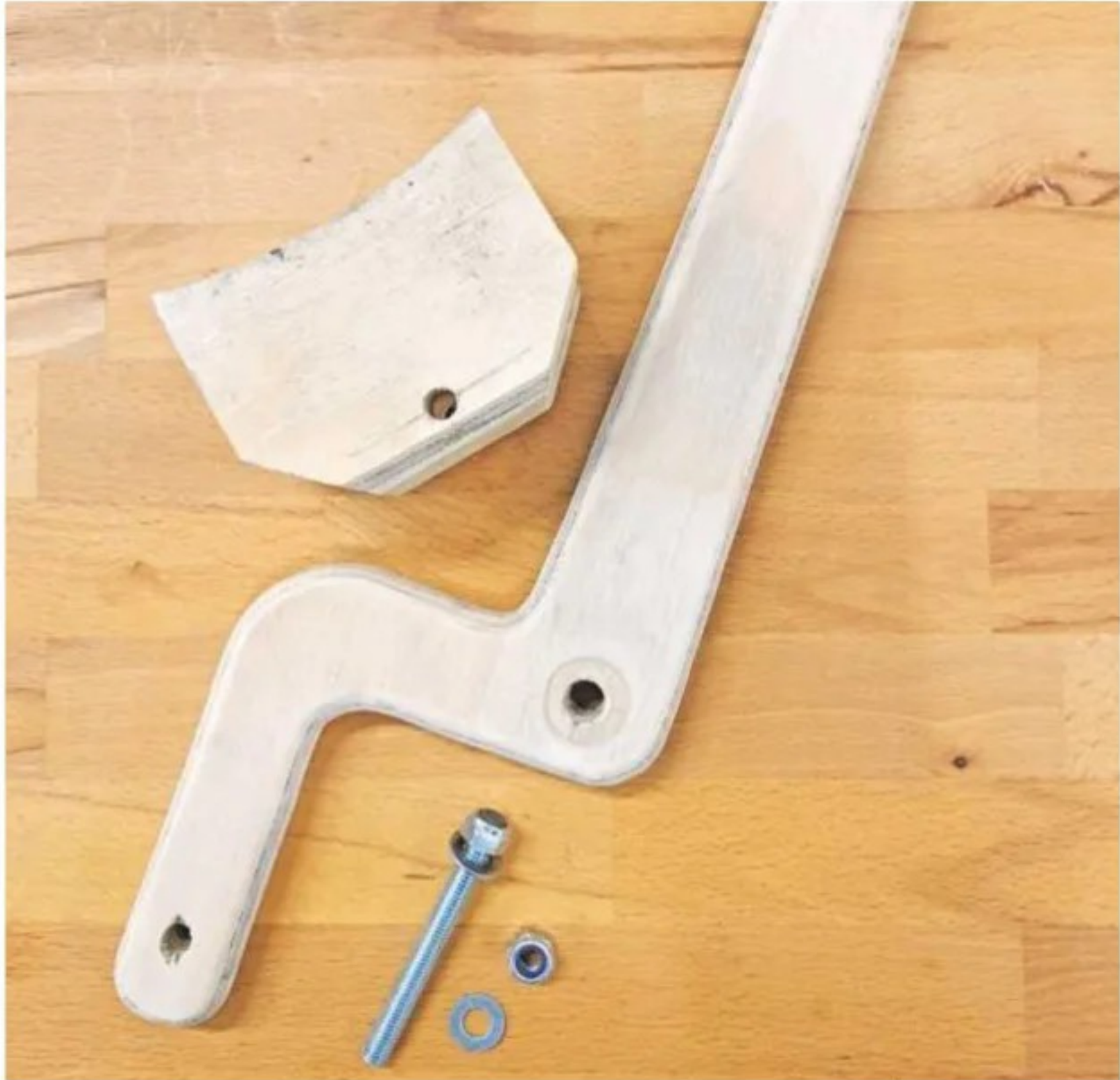
17 The brake is a simple block of wood, which acts on a single rear wheel
