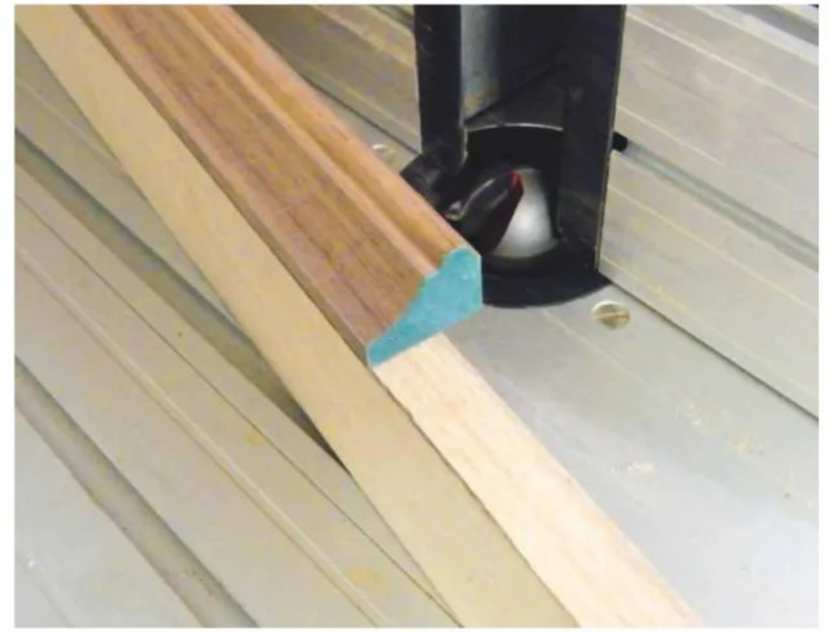
21 ... or stick the wood to be moulded to the edge of some scrap timber
