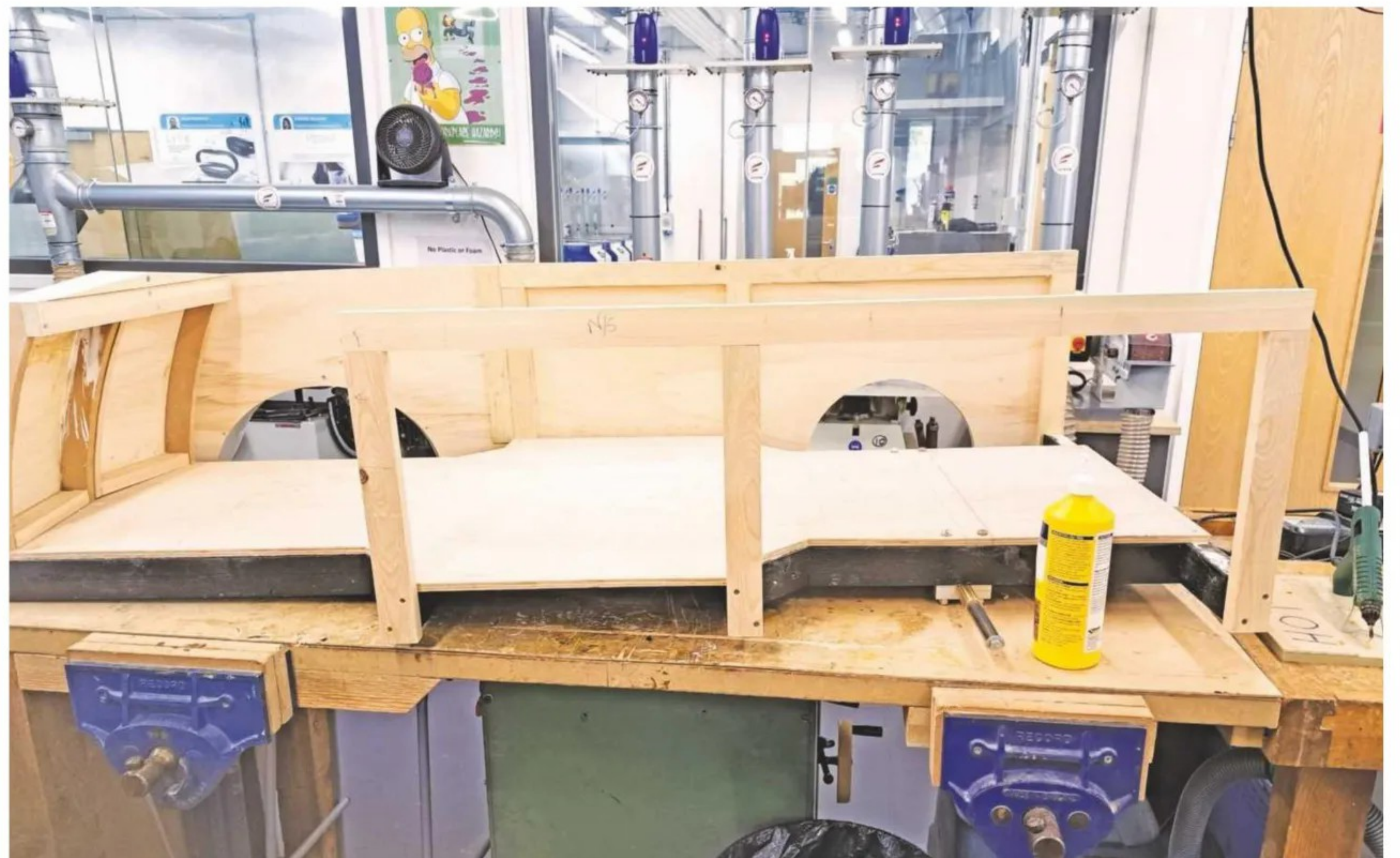
6 Flat panels are fixed to vertical pieces of 2x1
