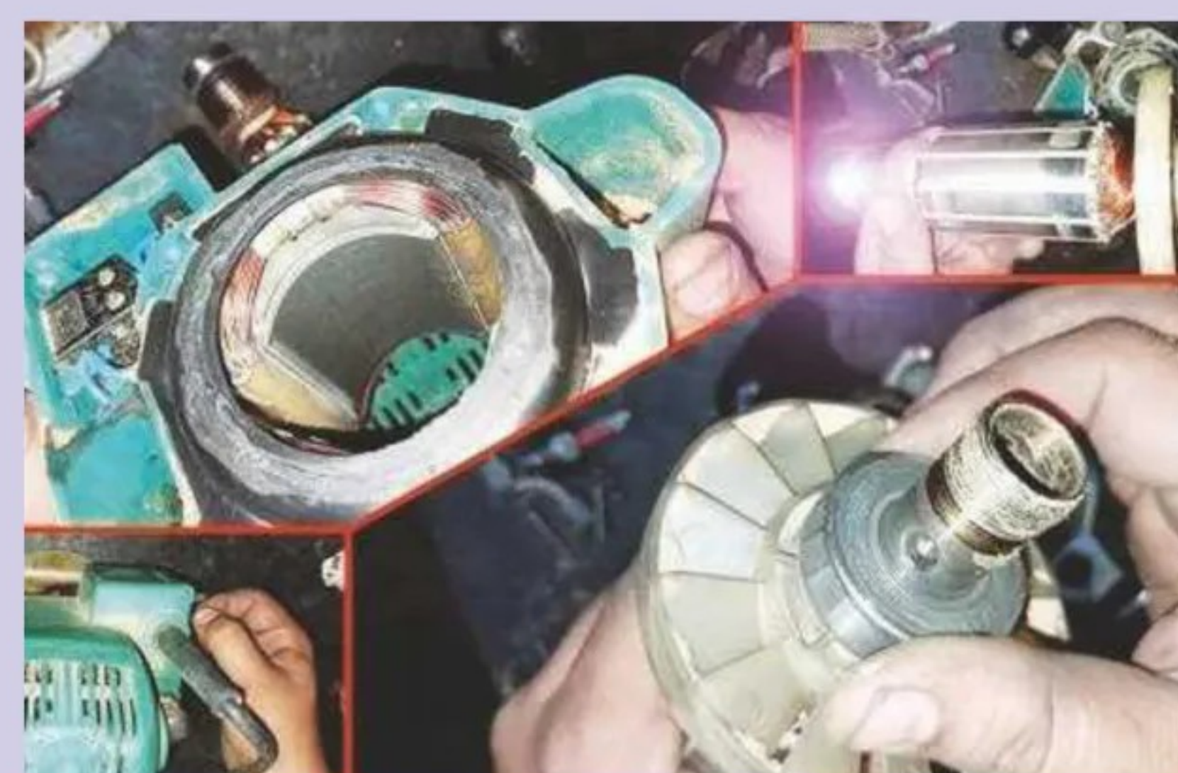
Router armature sparking
