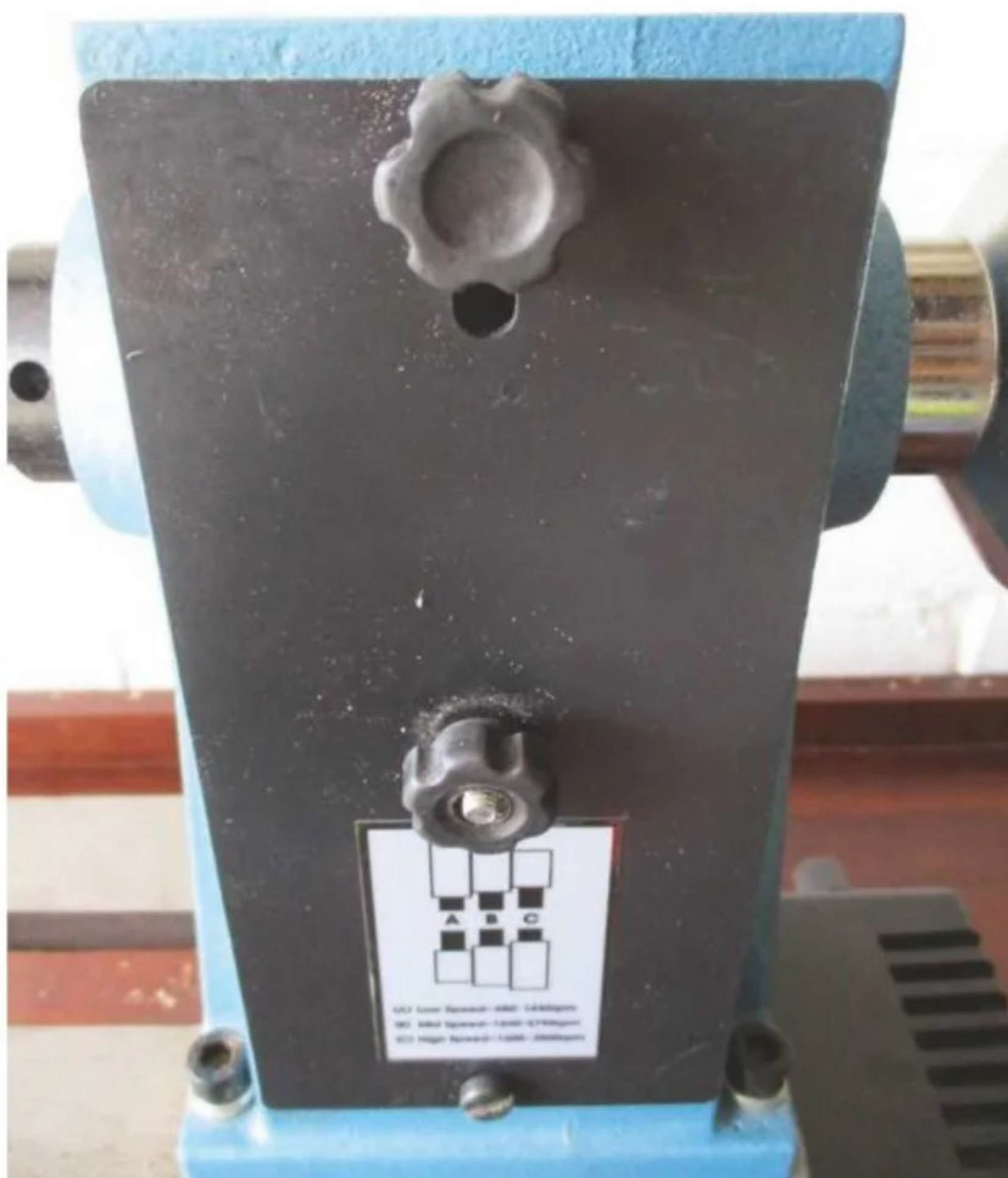
Access panel has no interlock or warning
