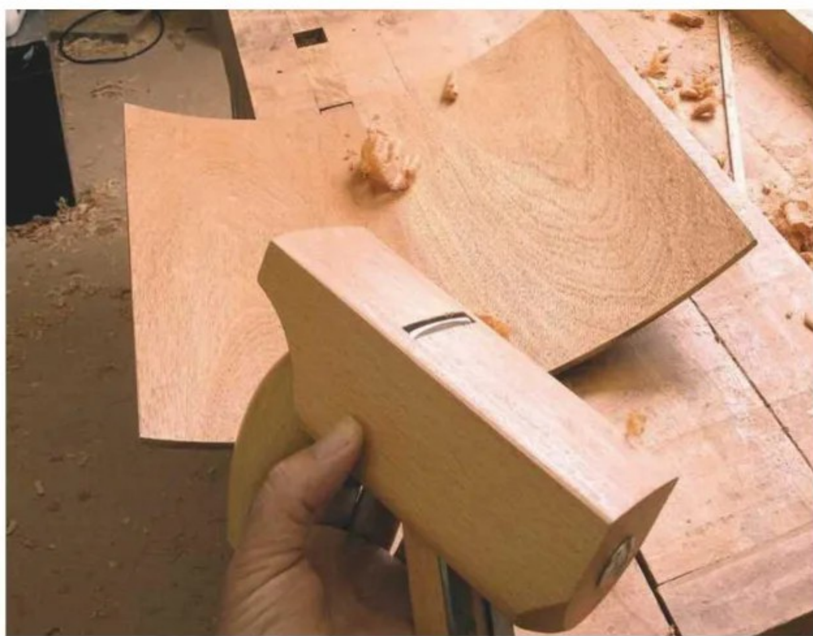
6 To smooth a curved panel's inner surface, here I'm using a reshaped wooden block plane
