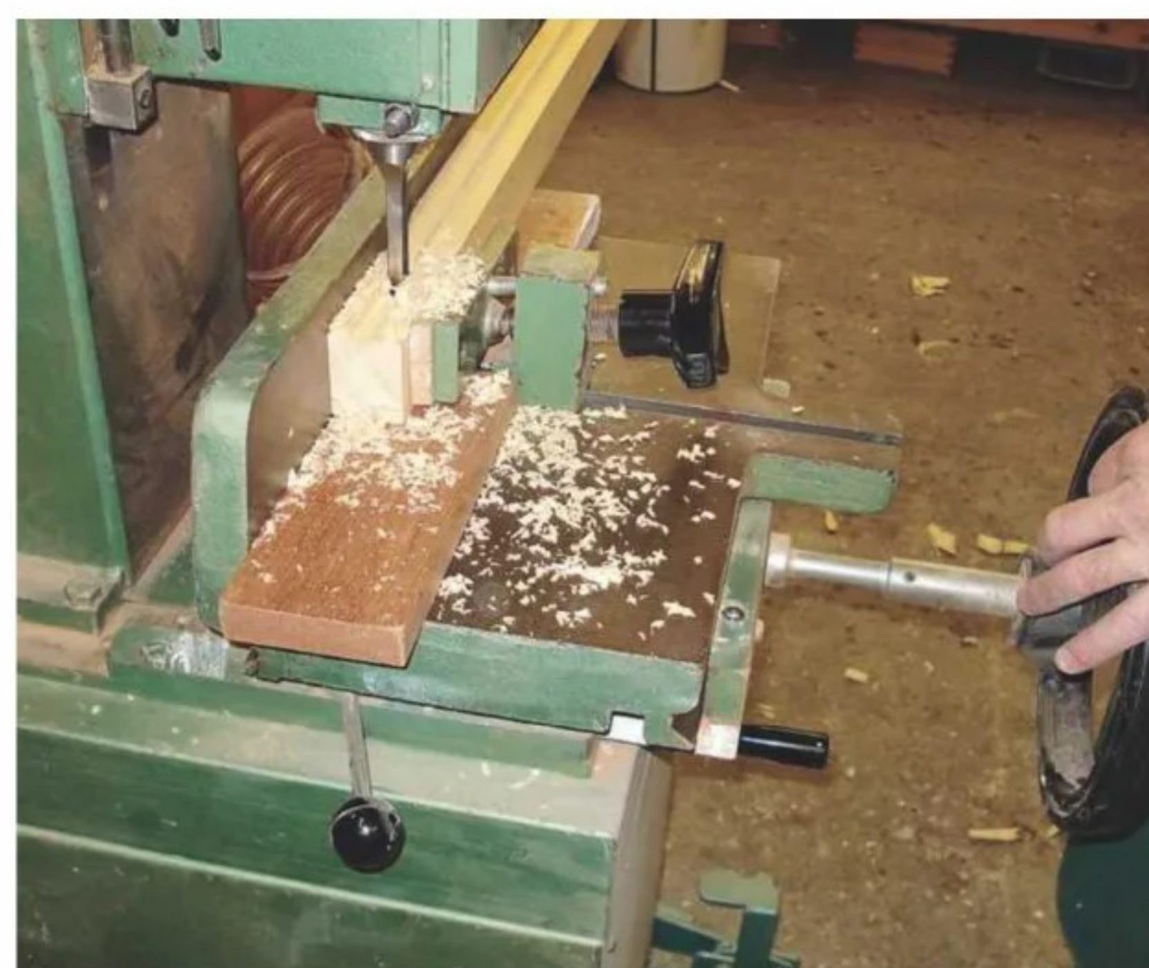
12 ... ready for mortising, a task that I carried out on, well... the mortising machine!
