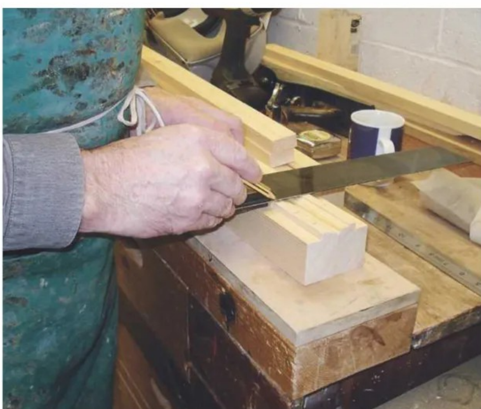
11 After planing and moulding stiles and rails, the stiles are marked...
