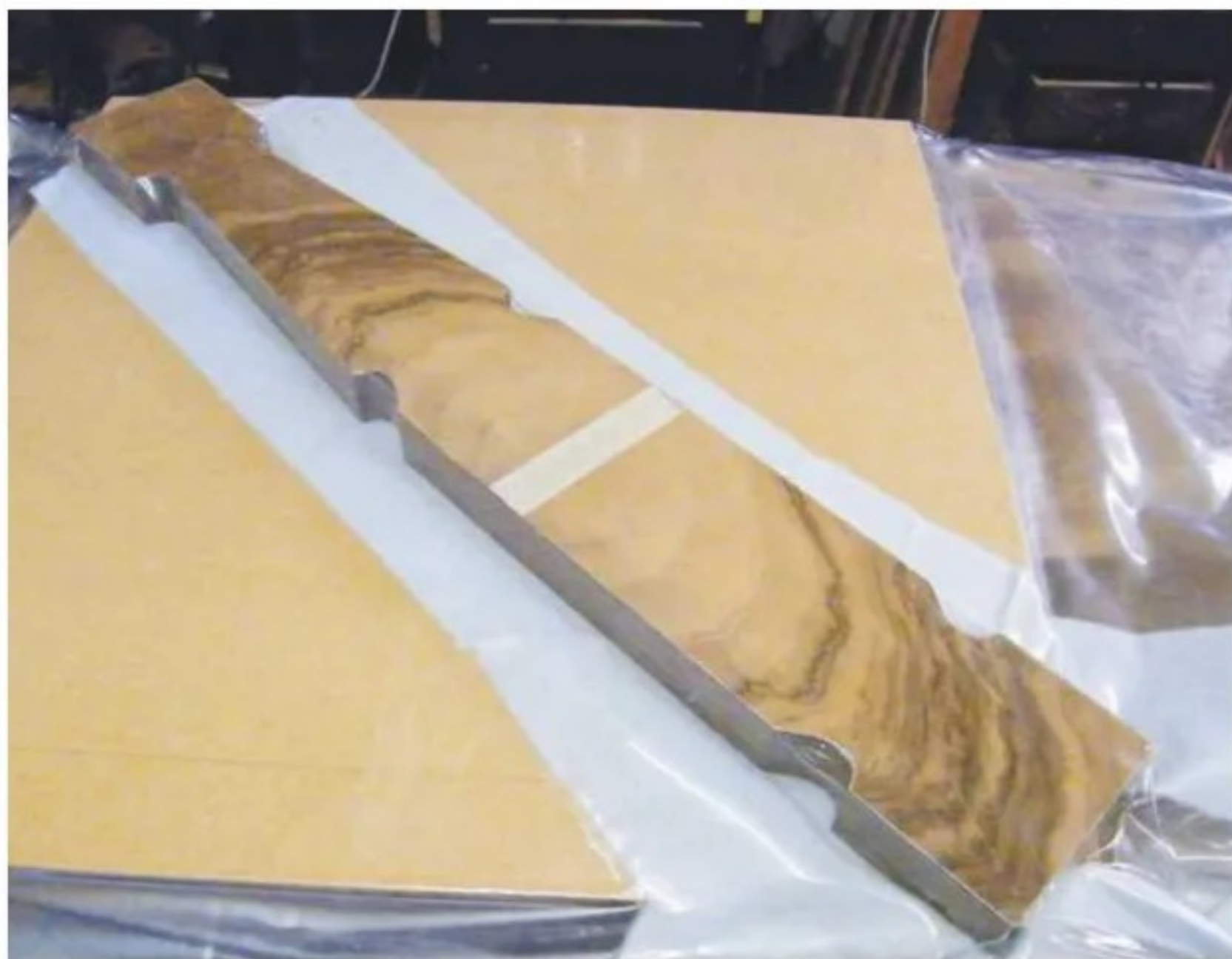
9 Glue the veneer to the column's face – I used a vacuum press here
