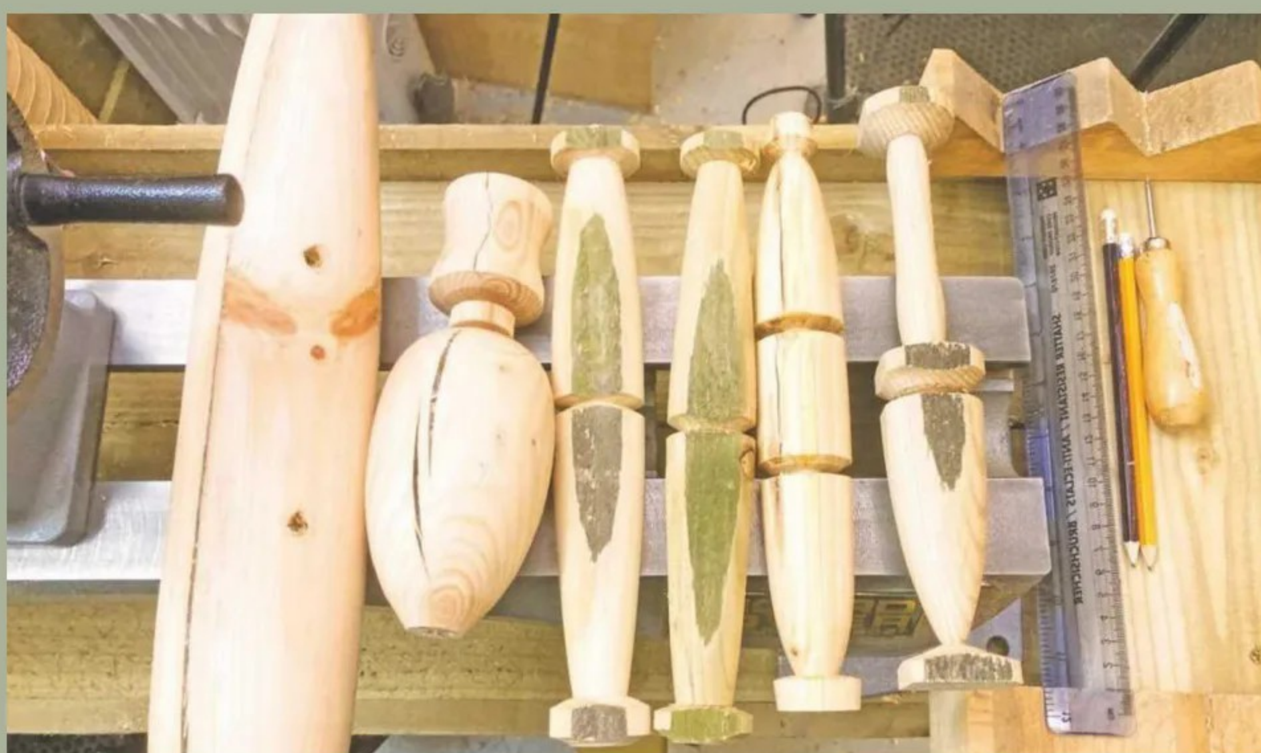
19 Having completed each of the components, I cut them up using a pull saw along with a bench hook
