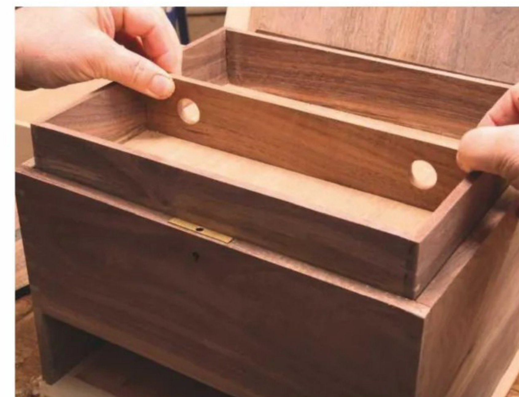
10 Thanks to the piston-fit, when let go, this tray sinks slowly into position as air escapes around it
