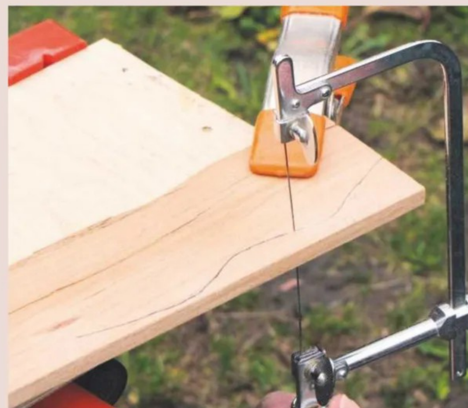
3 When fitting a new blade, ensure teeth are pointing down towards the handle. Doing so keeps it under tension while sawing
