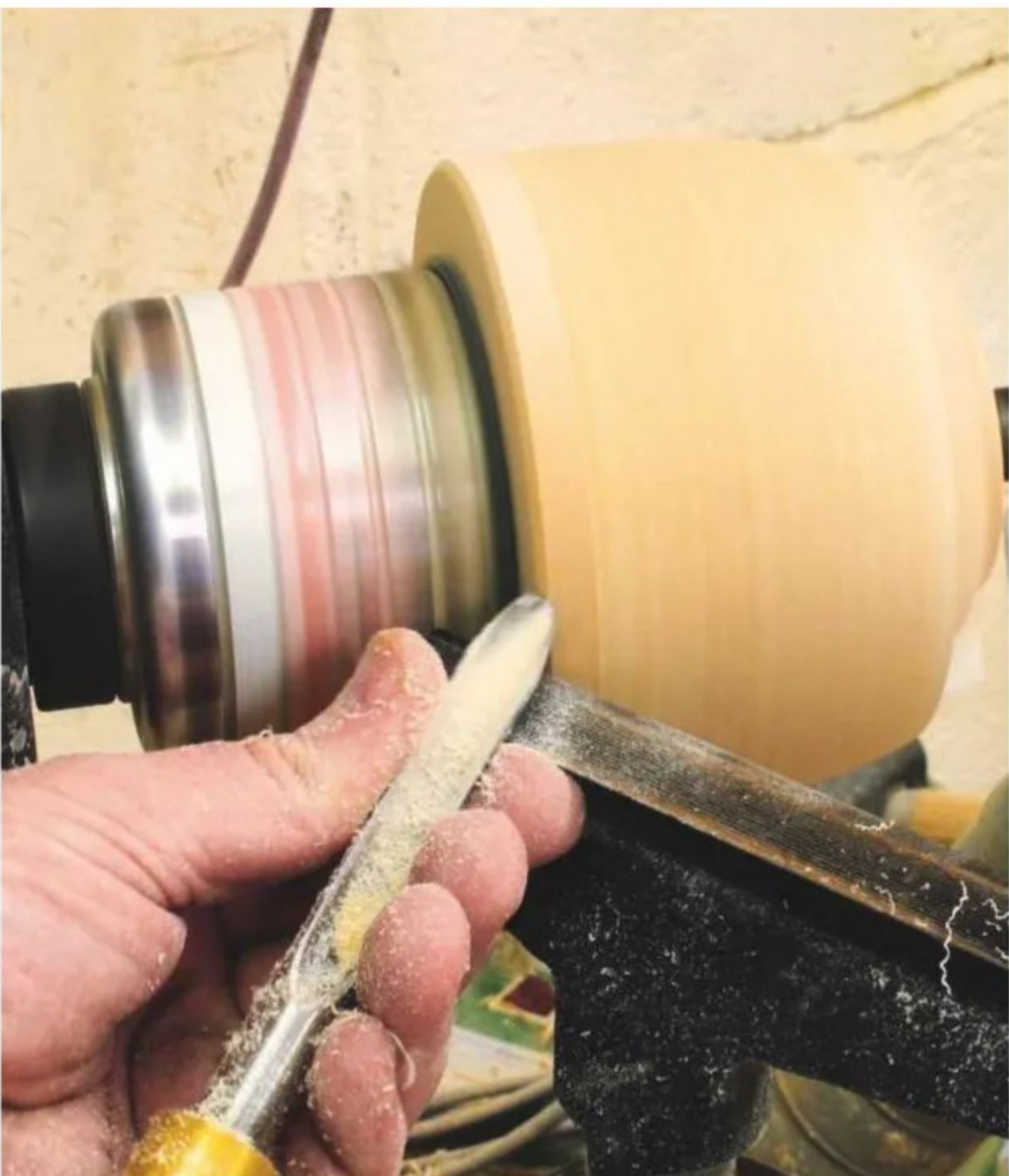
29 Here I'm just lightly rounding over the lid's edge. If you're not confident using the gouge, 120 grit abrasive will do a suitable job
