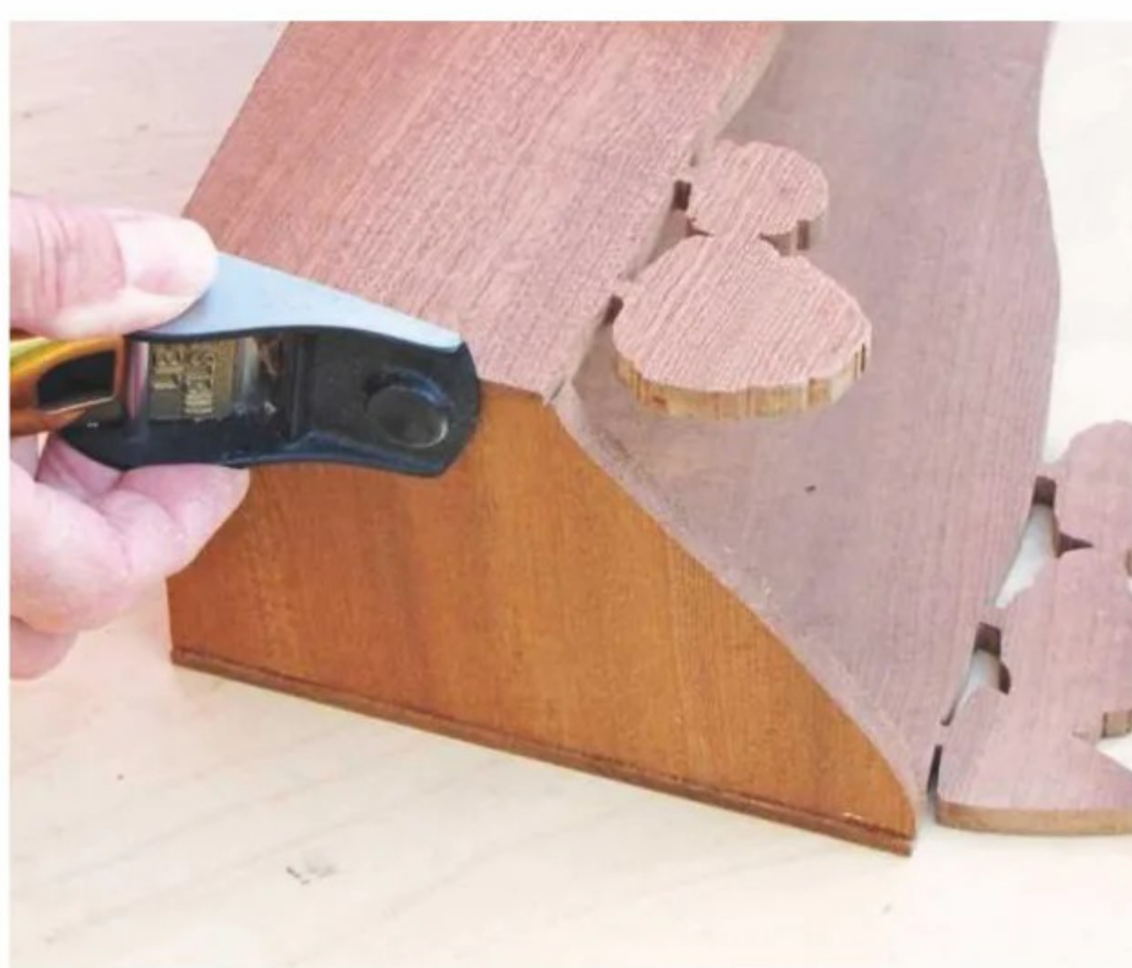
14 When the glue has dried, carefully trim excess end-grain on the corner joints
