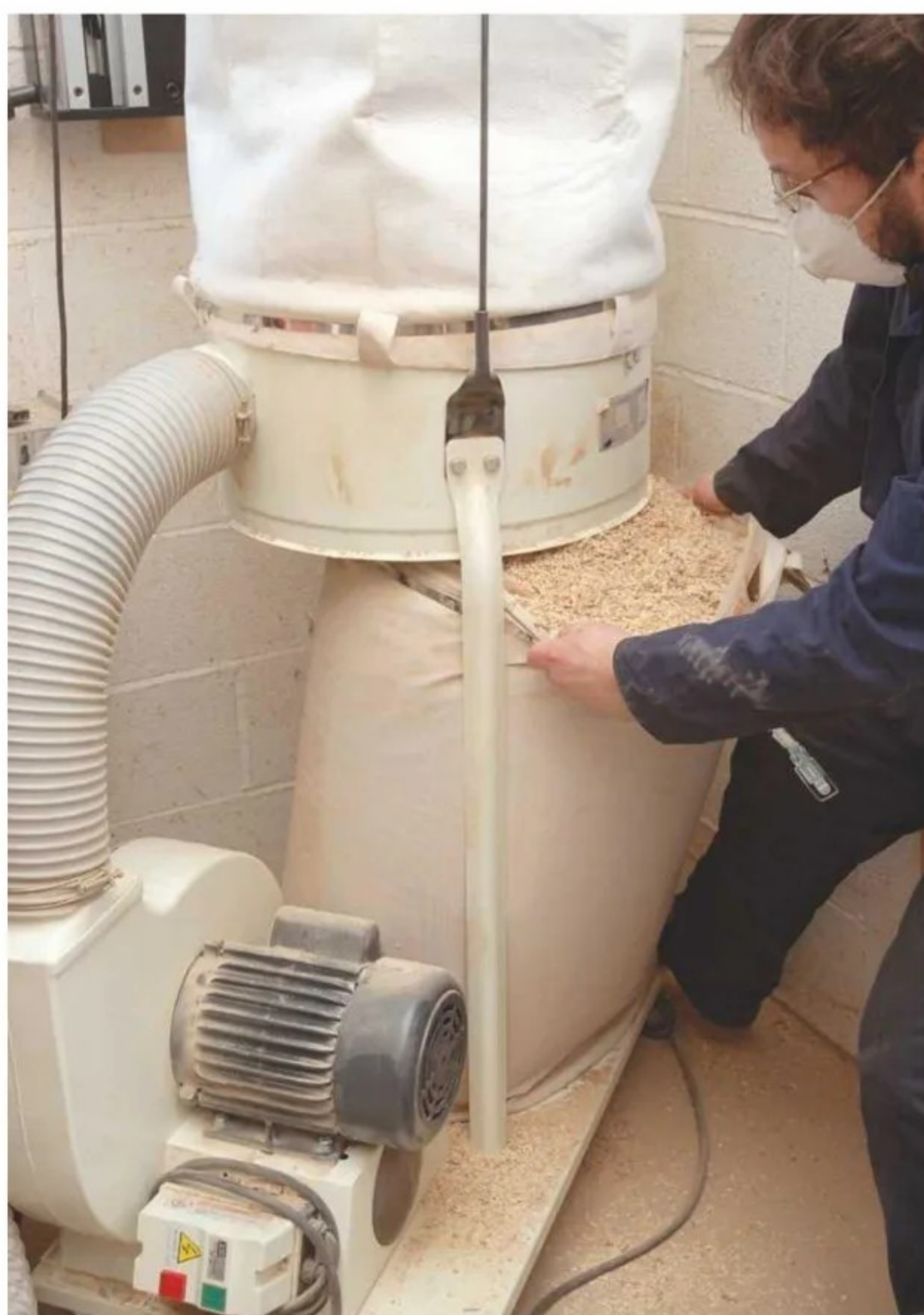
13 Allowing a collection bag to overfill as shown here makes changing it more difficult
