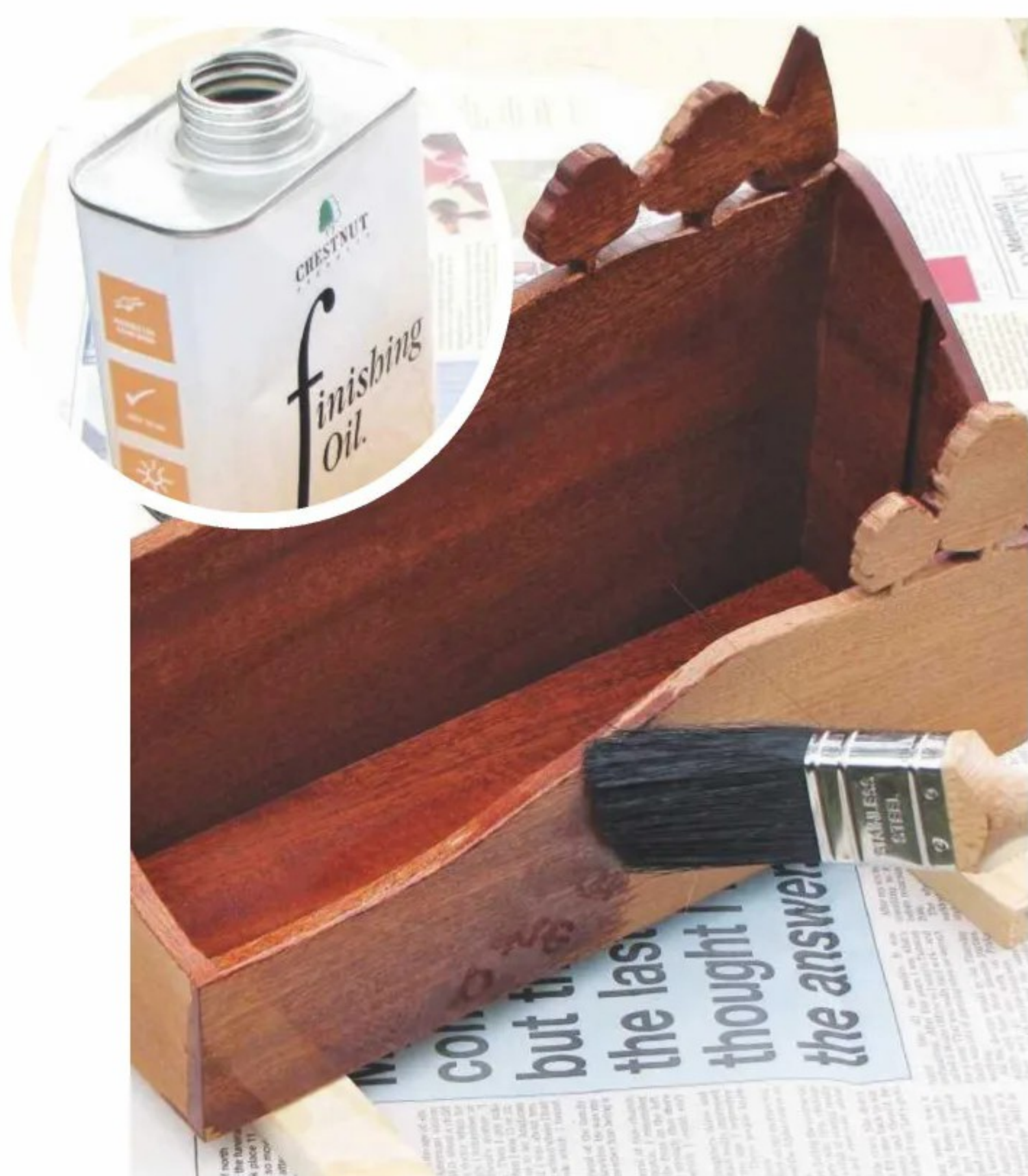
19 After final sanding, brush on two coats of Chestnut Finishing Oil. Denib and complete with wax polish
