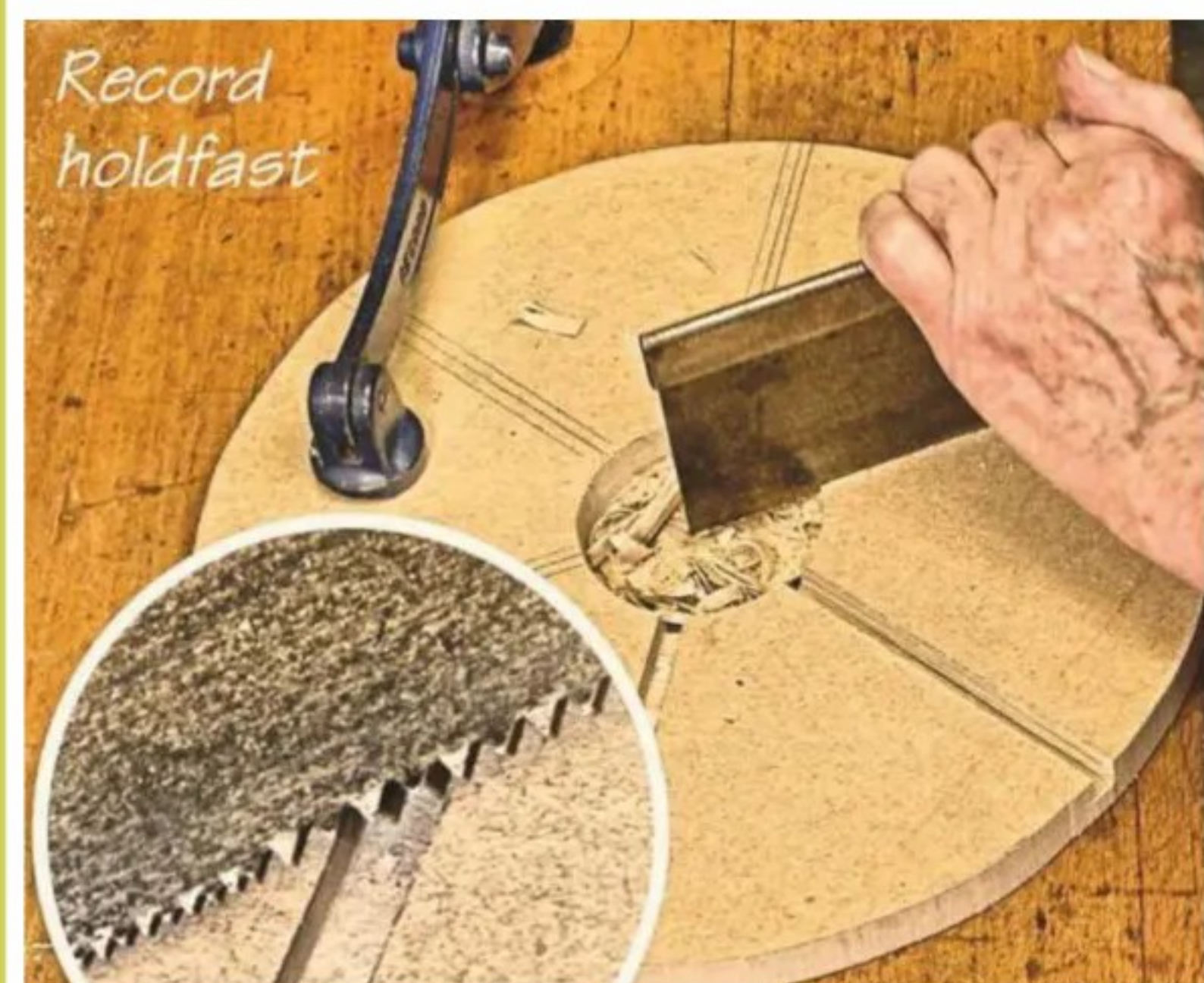
8 The coarse teeth of my graduated-toothed tenon saw soon deepened the groove's sides
