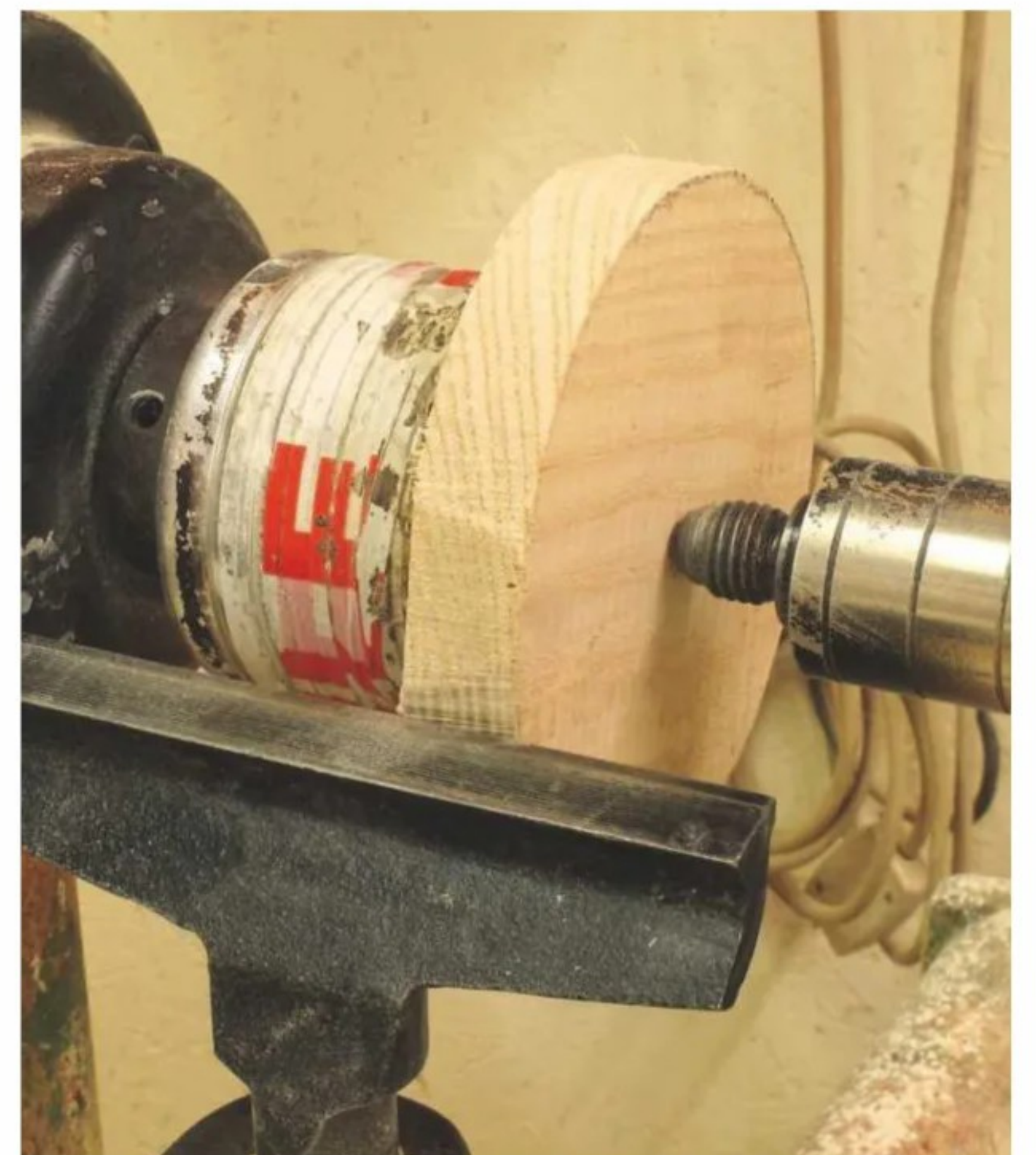
25 The lids are turned using a vacuum chuck; the side that'll become the top is sanded flat and mounted on a drum chuck
