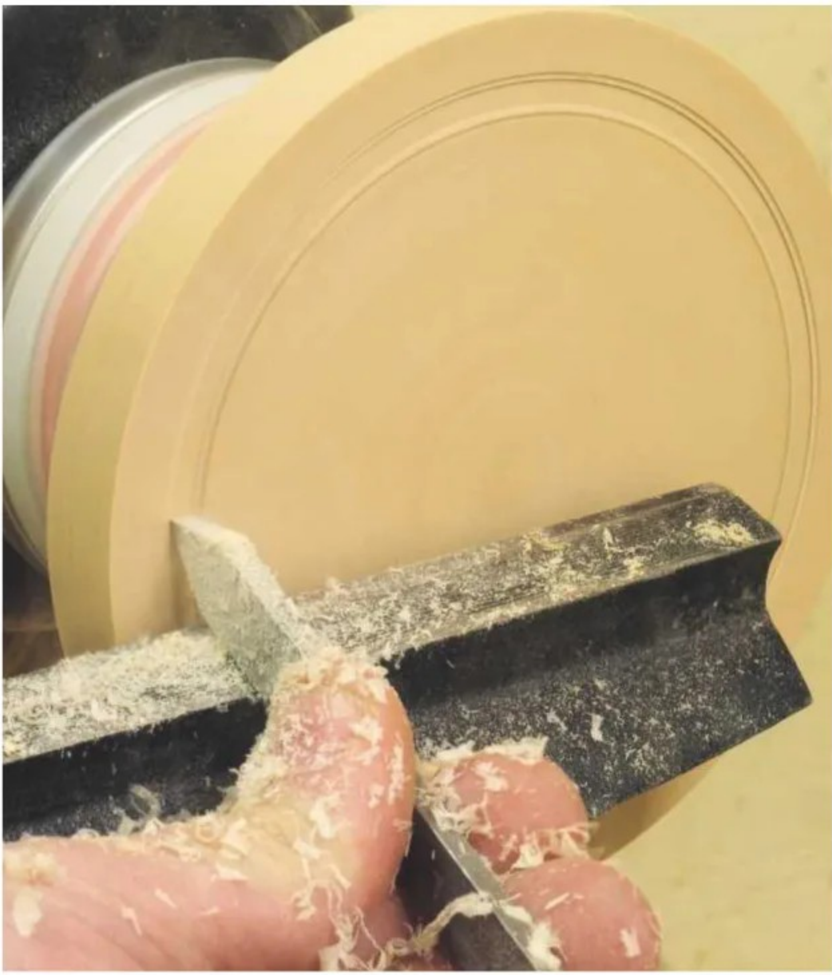
26 Once turned to a circle, measure and cut the spigot to fit into the bowl. Don't make side-grain boxes with a tight-fitting lid, as even slight warping will cause it to not fit
