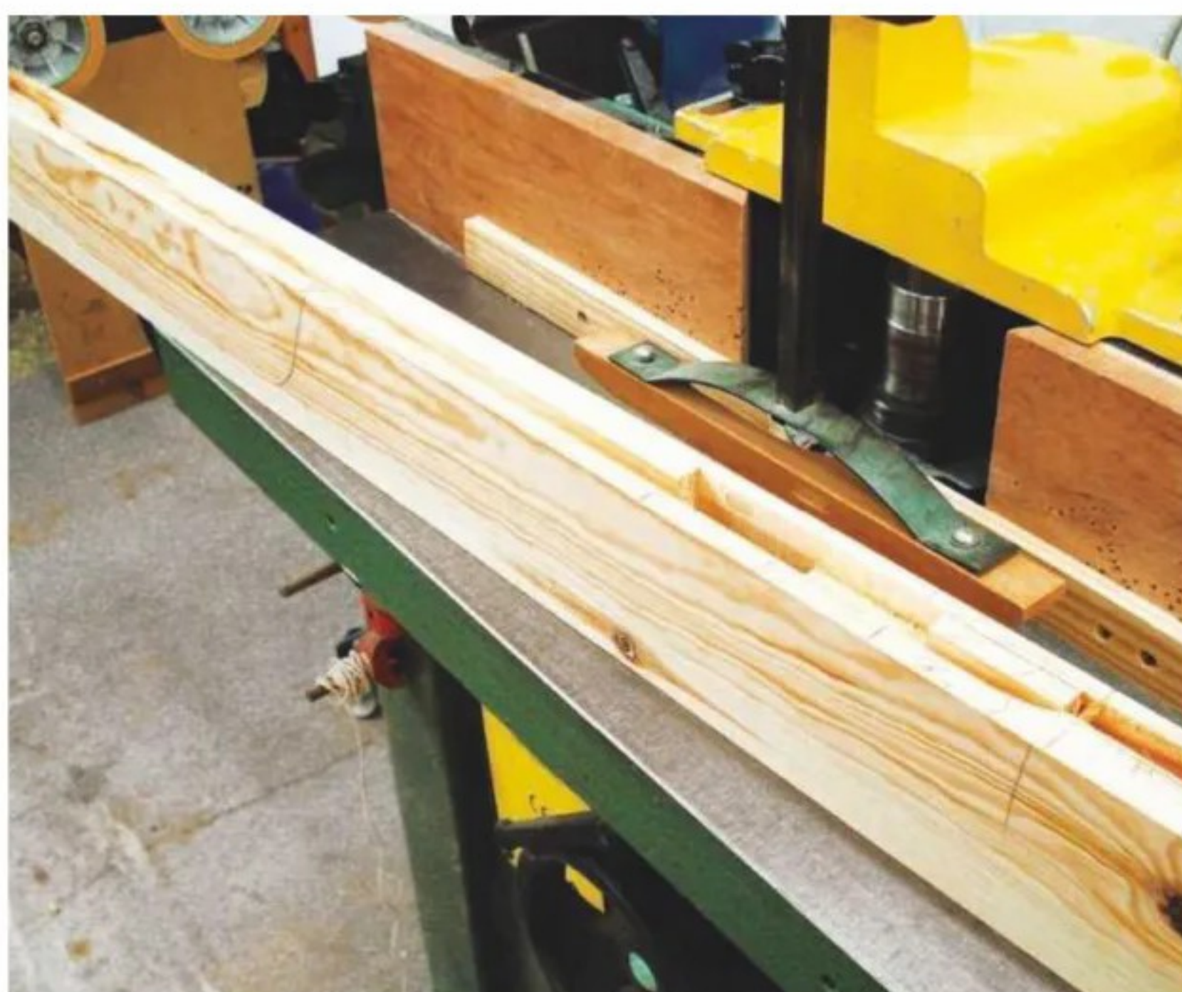
10 A wobble saw was used to cut grooves in the stiles...
