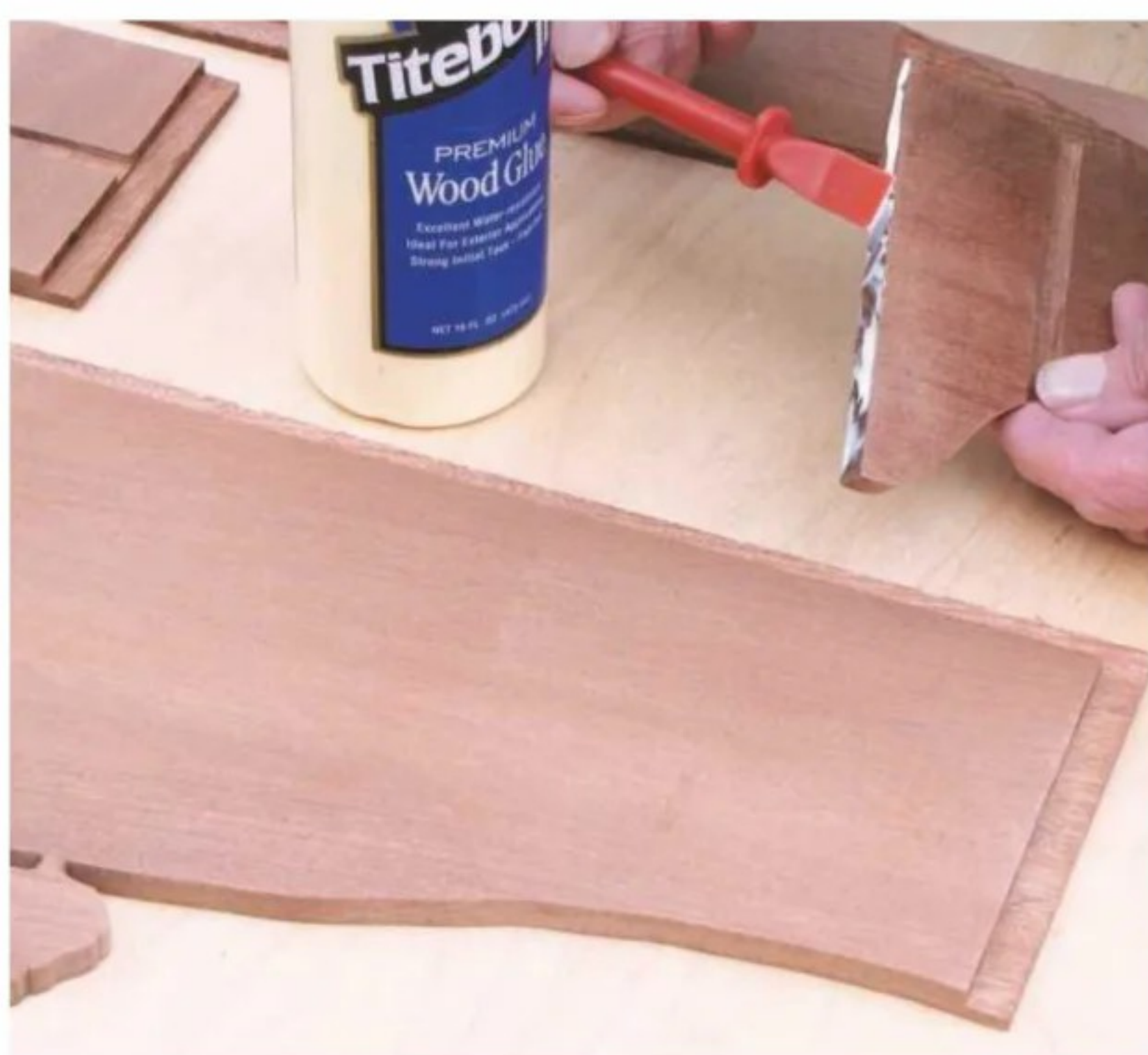
11 Check the ends fit neatly into rebates on both front and back panels. Apply PVA glue sparingly
