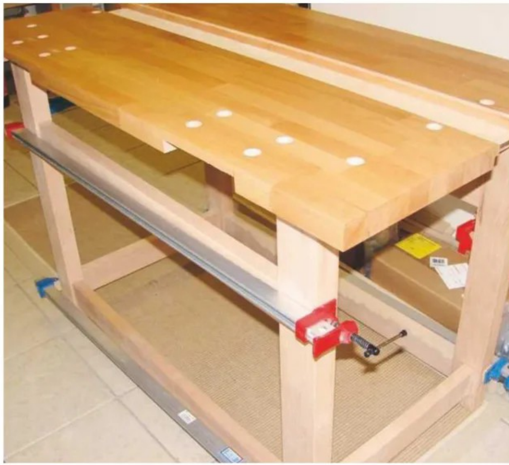
8 The bench top in dry assembly together with bench framework
