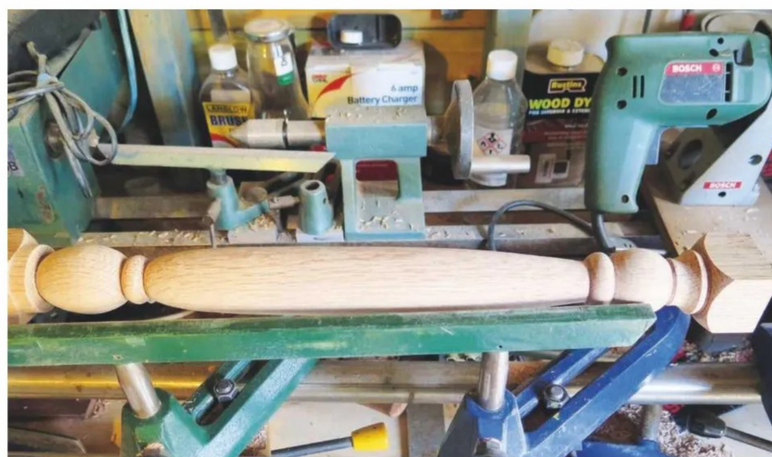
2 One of the turned columns prior to splitting
