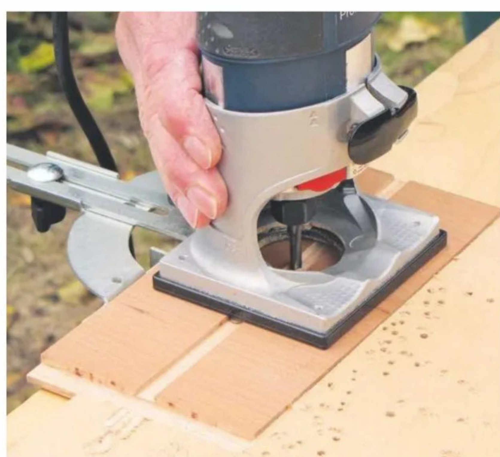
7 On both end pieces, rout through grooves to a depth of 3mm. A simple jig holds these in place
