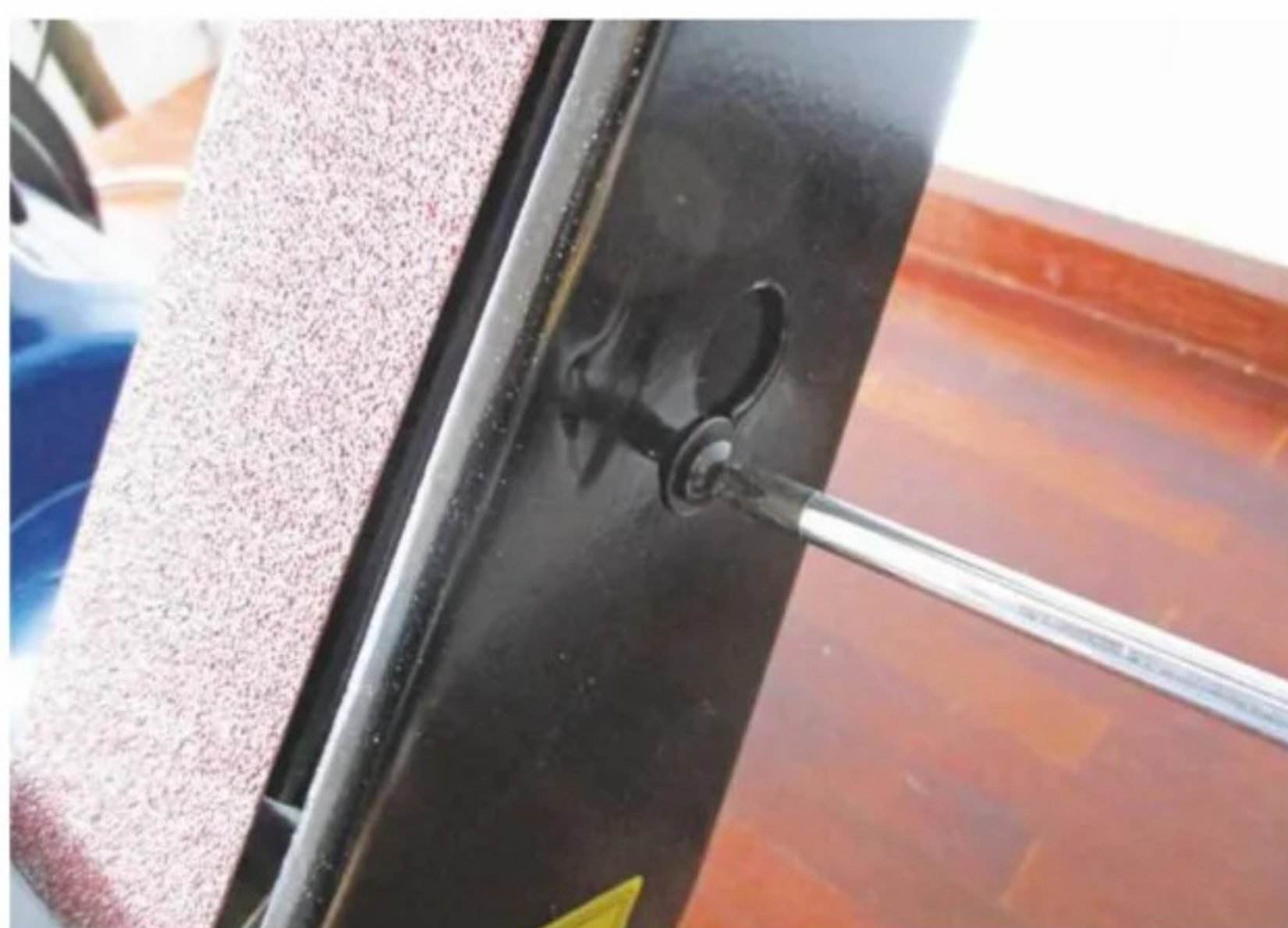
There's only one screw to undo on the belt cover
