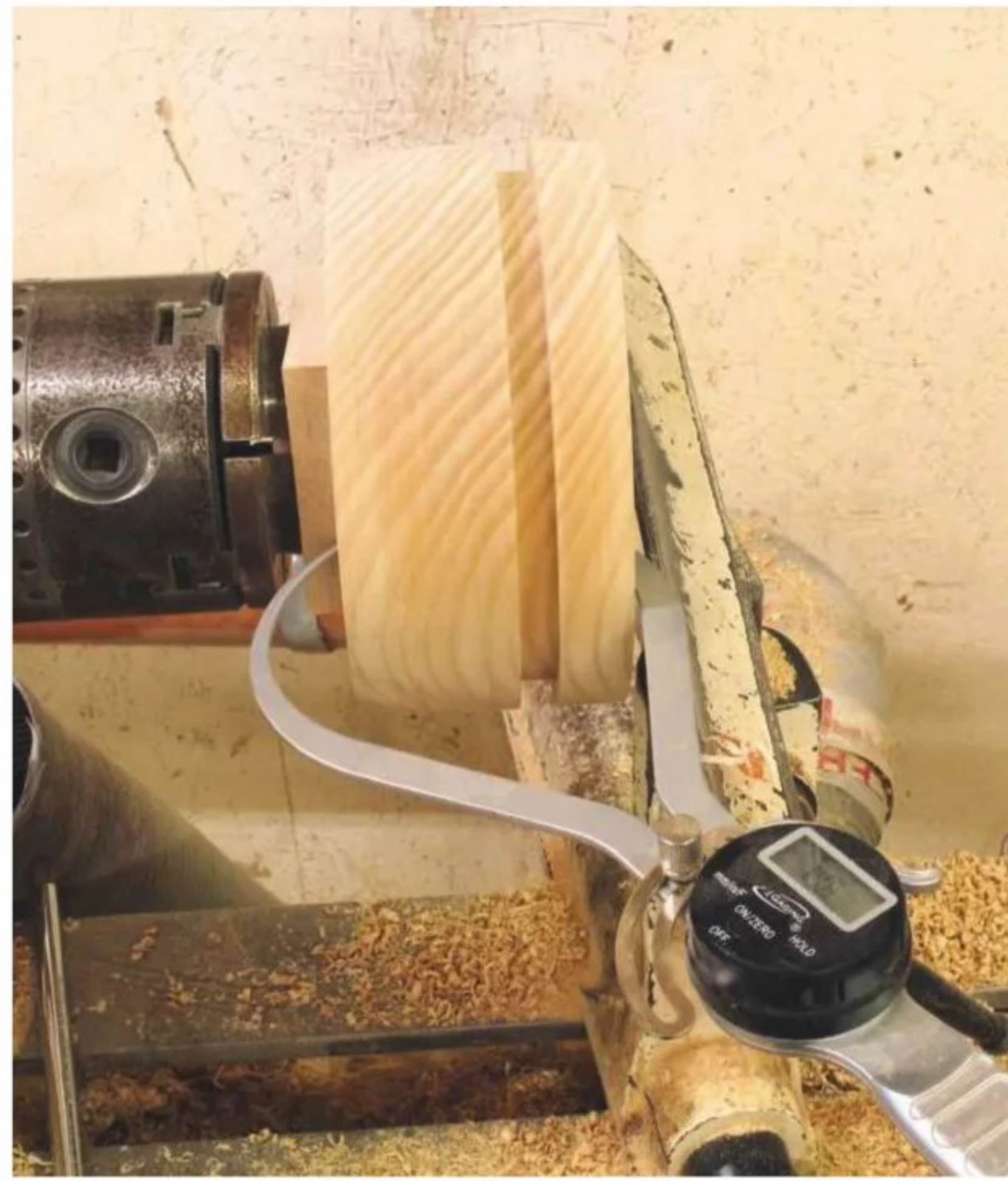
18 Use a pair of digital callipers to check the base thickness; a bowl will always appear deeper than it really is, so ensure to check this frequently
