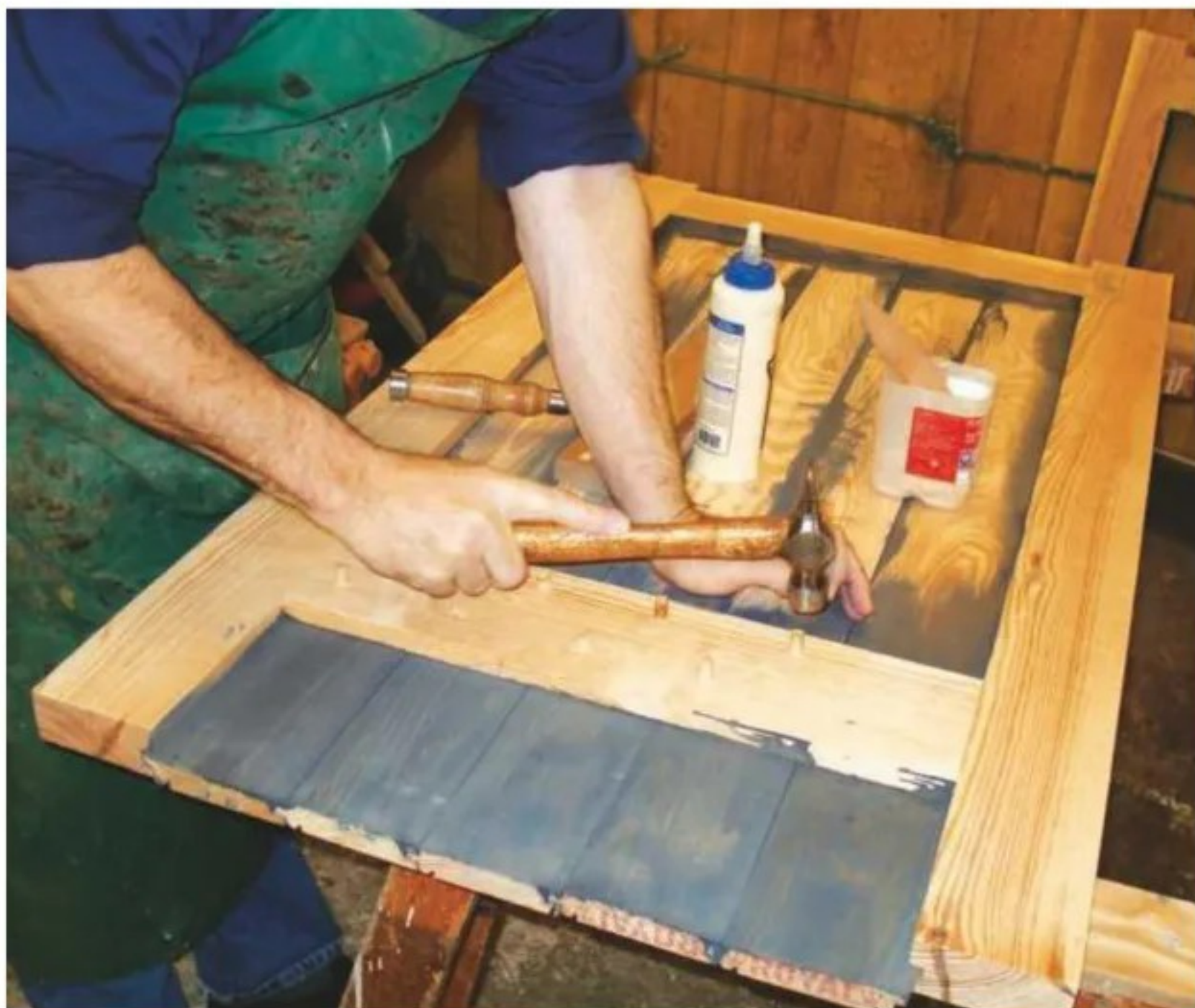
15 ... then secured by screws, which were concealed with pellets made from offcuts
