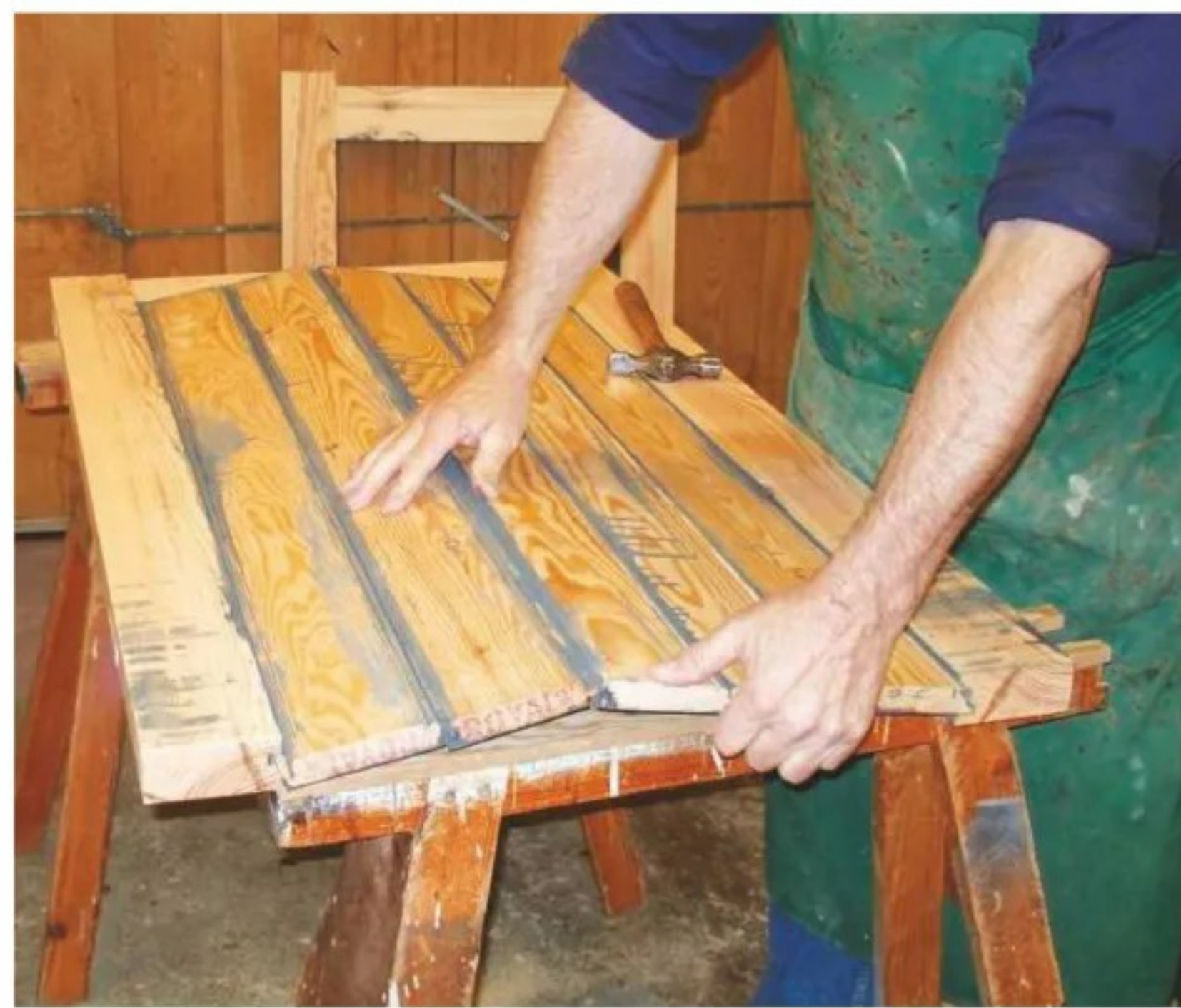
14 Boards are sprung into place between the stiles...
