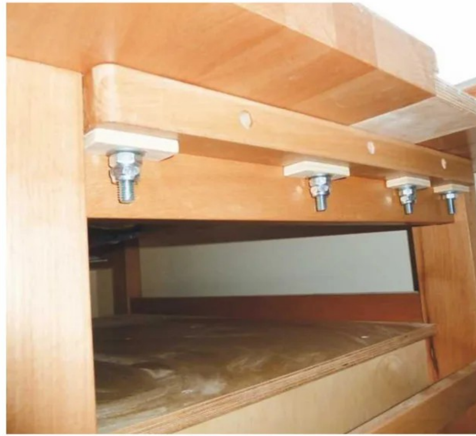
9 M10 bolts are the linchpins behind the bench's top-to-rails construction
