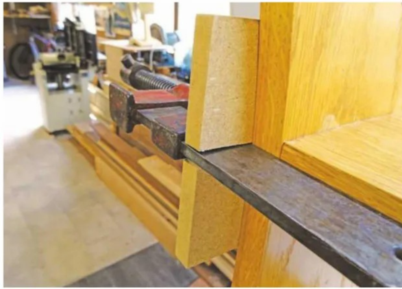
5 Use of scrap wood alternative for gluing up a furniture carcass
