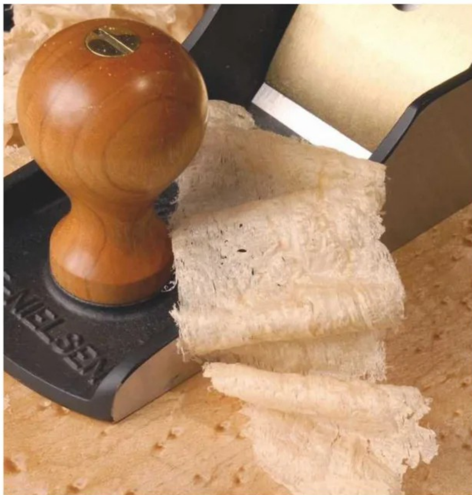
1 A well-adjusted hand plane is a lovely tool to use, which is largely due to the beautiful thin, dust-free shavings produced
