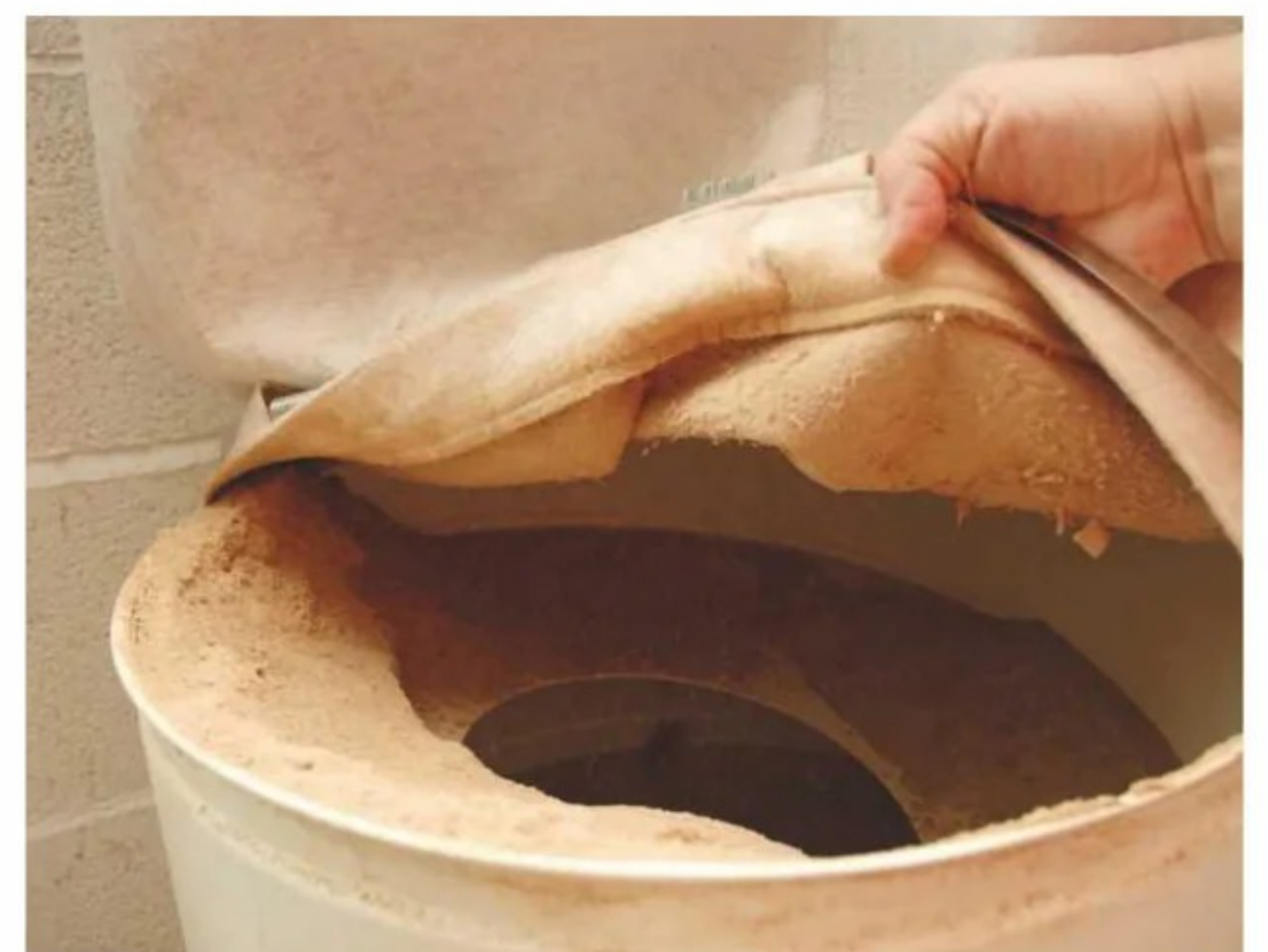
11 Dust accumulating in the air filtration bag cuts down efficiency by reducing airflow
