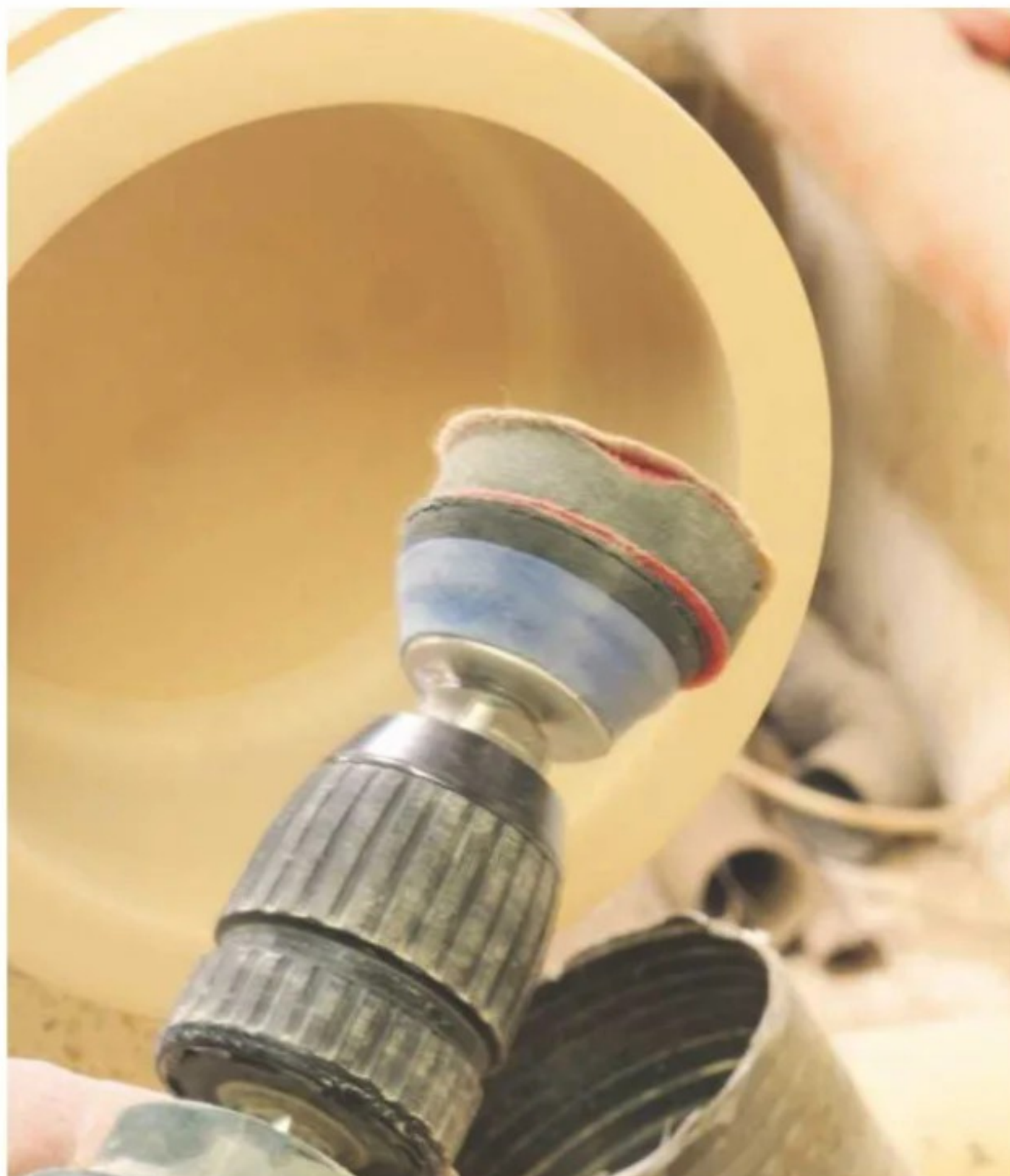
20 Owing to the interior's shape, I'm using soft Simon Hope interface pads, which should better mould to the shape
