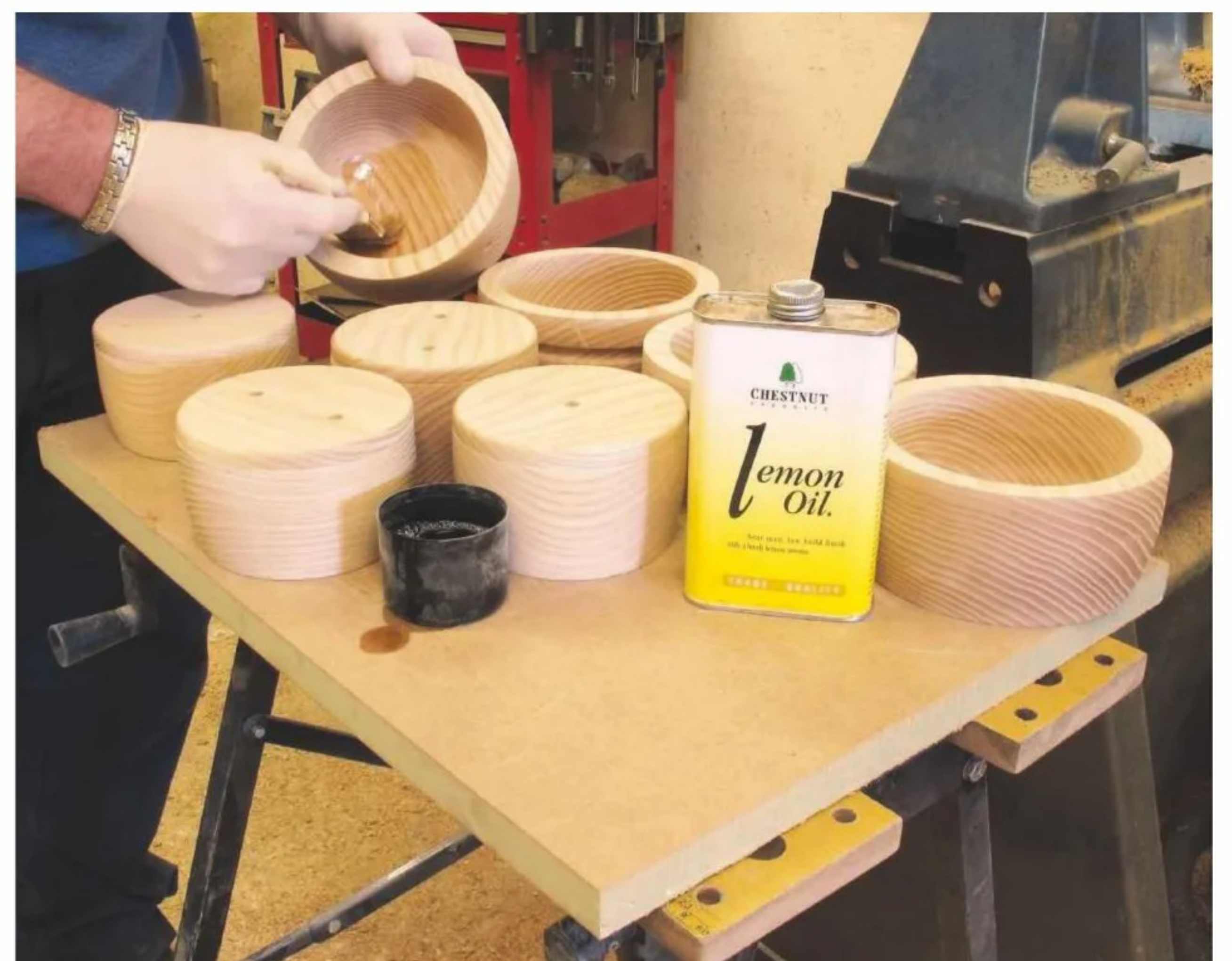
33 With no gloss required, a matt finish such as lemon oil produces a durable result; two coats with a light rub down between each is perfect ✕
