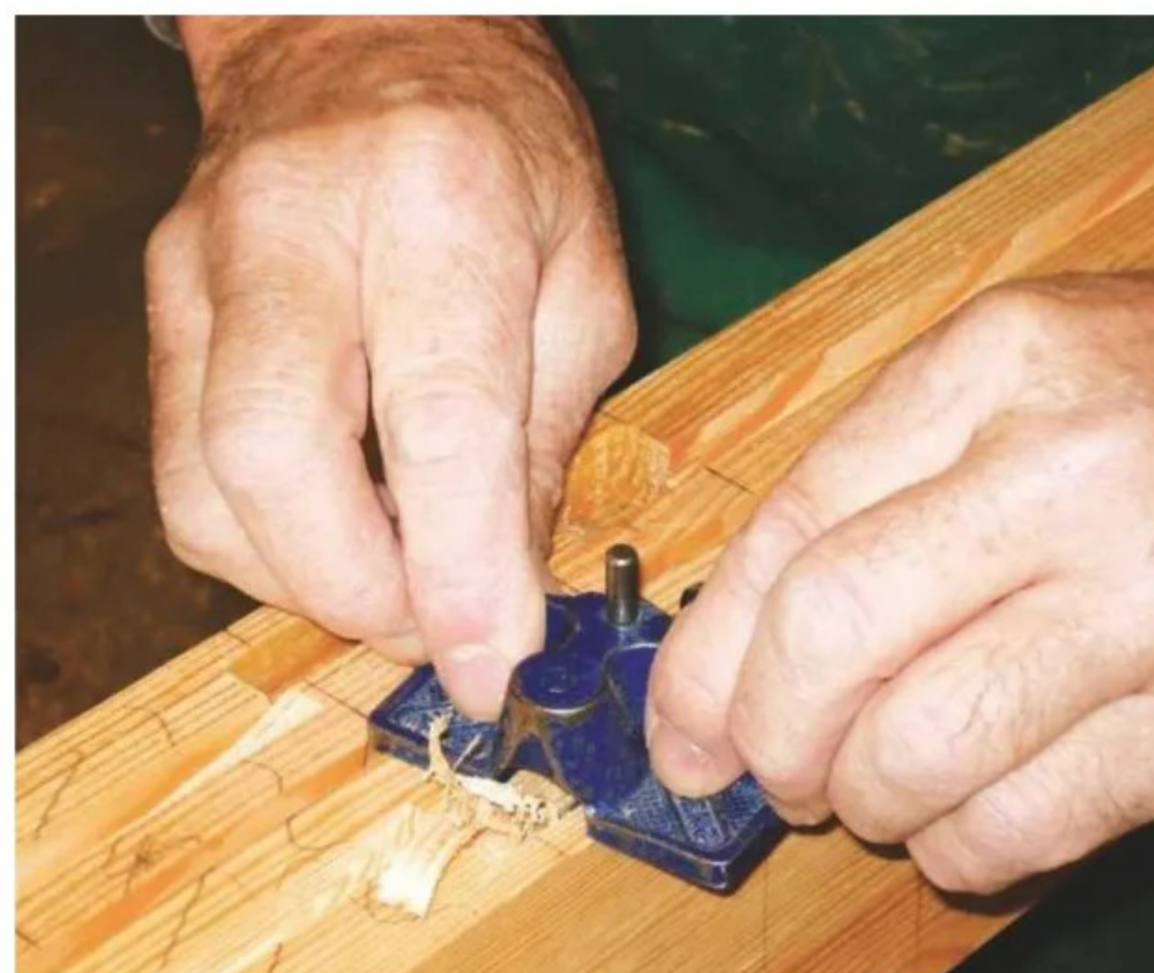
11 ...while a hand router is ideal for cleaning up the haunchings' bottoms
