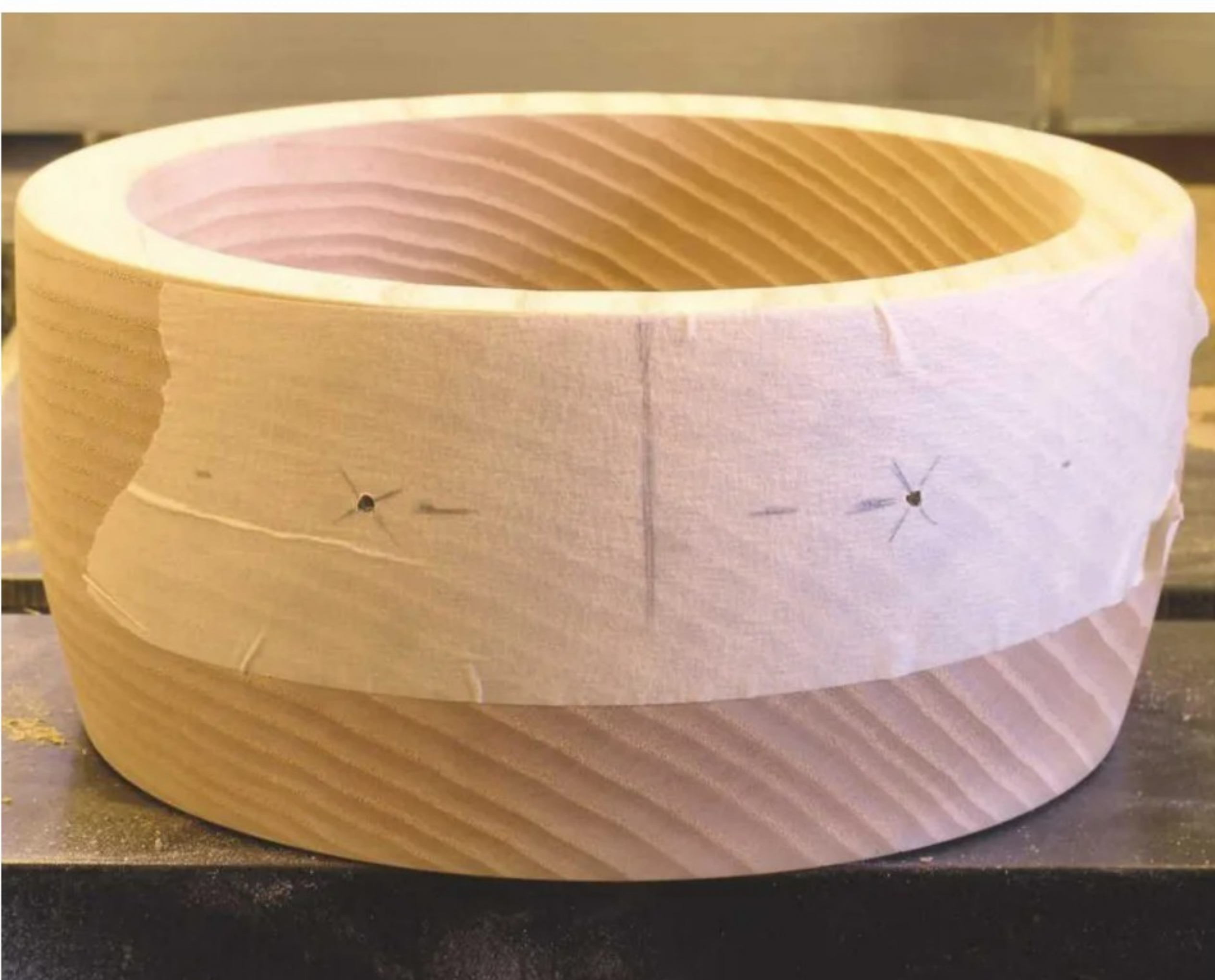
32 Two of the un-lidded bowls have two holes, so that a rope handle can be attached. These are marked on the side after applying masking tape to the piece, which prevents any scratching
