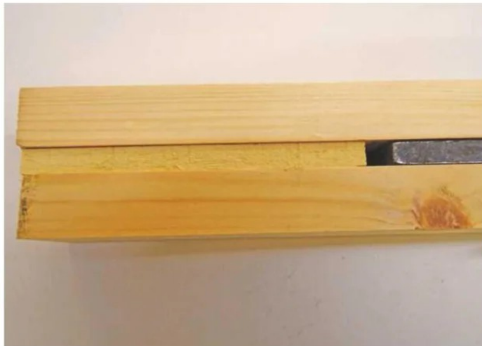
8 Wood spacer placed between extended pieces to match the cramp shaft's width
