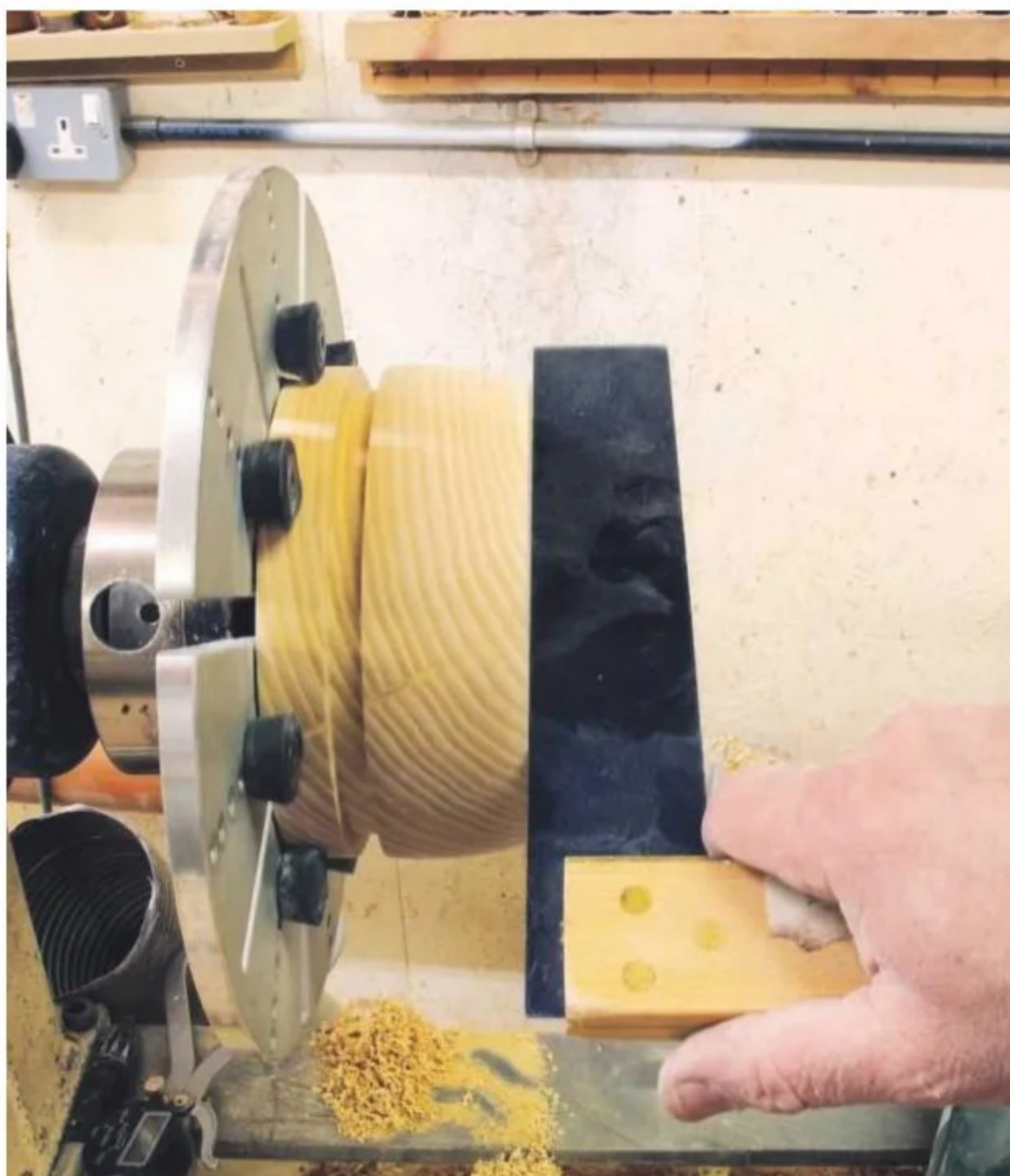
23 The bottom needs to be flat or slightly convex, so check this with a simple straightedge
