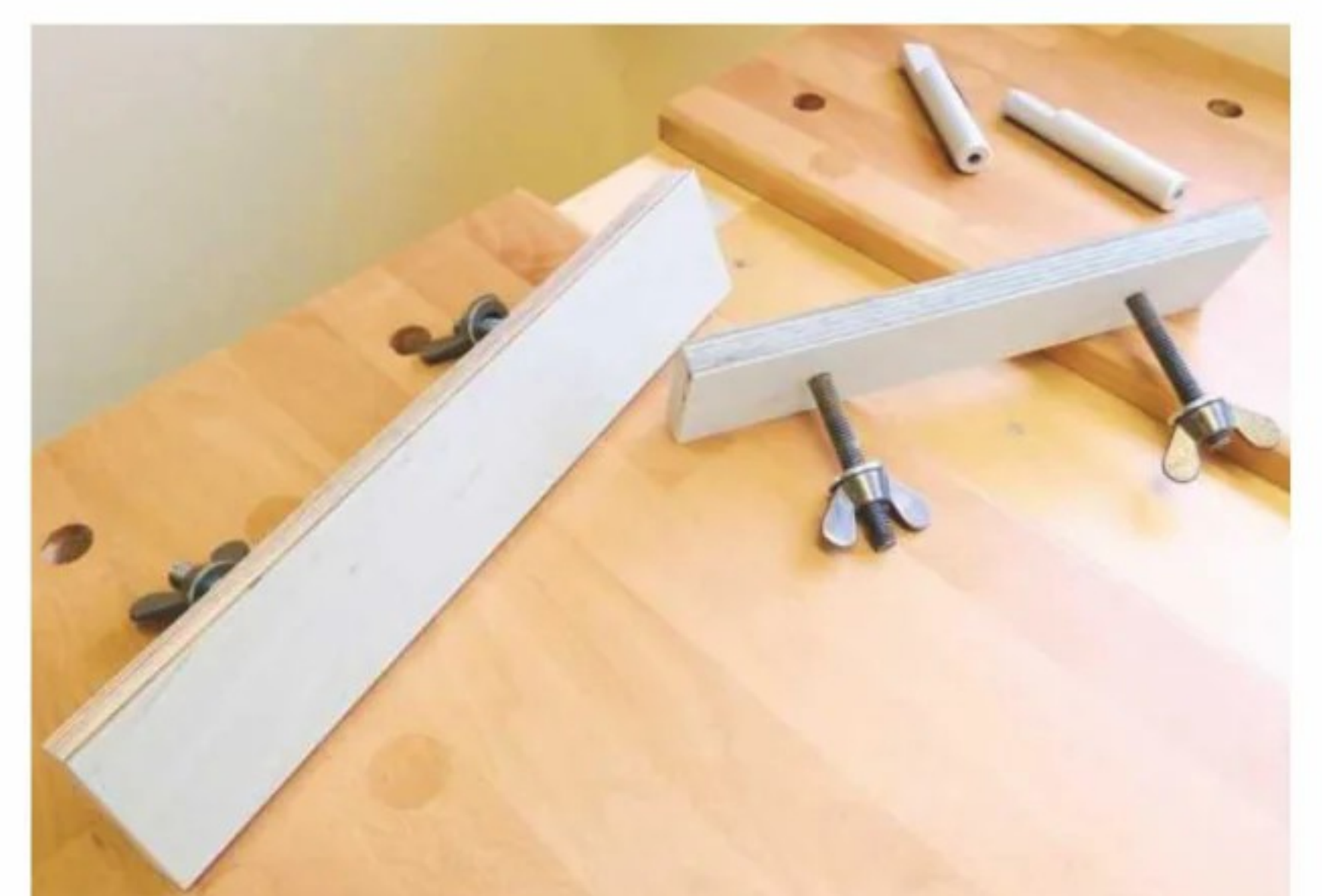
12 ... including 19mm dog holes for clamping work
