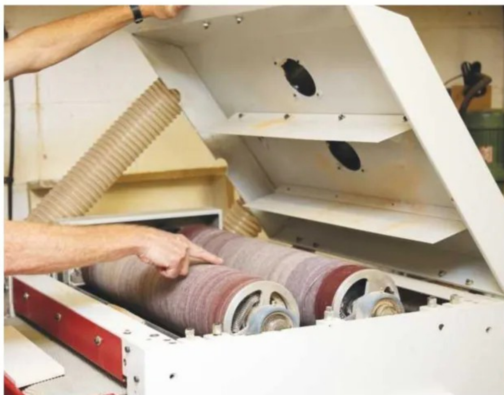
7 This dual-drum sanding machine produces dust very quickly
