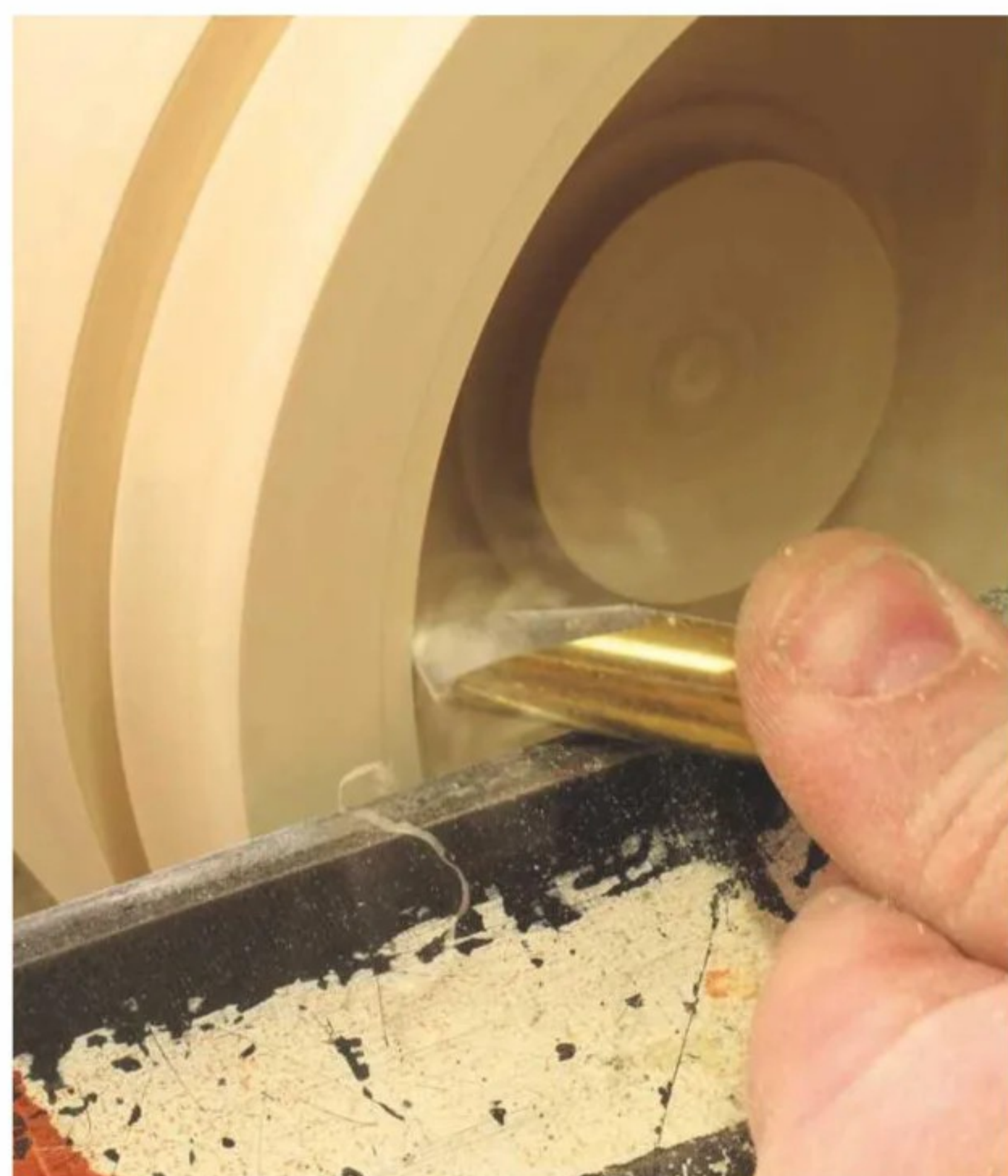
15 As the initial interior part is straight, when approaching the edge, I place the bevel at right angles to the work; this ensures correct direction of cut
