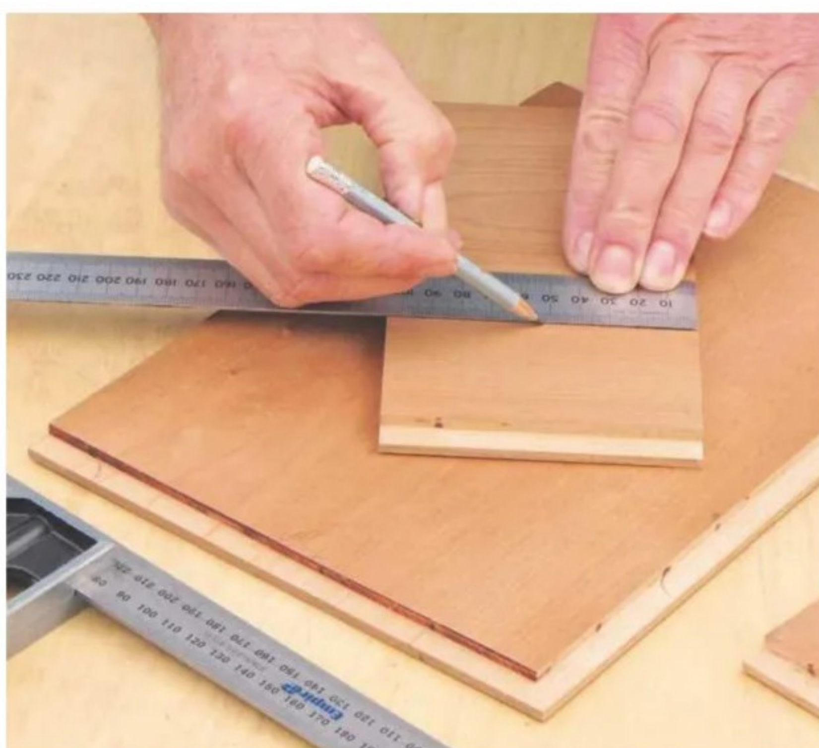
5 On both end pieces, carefully mark out groove positions for the divider panel
