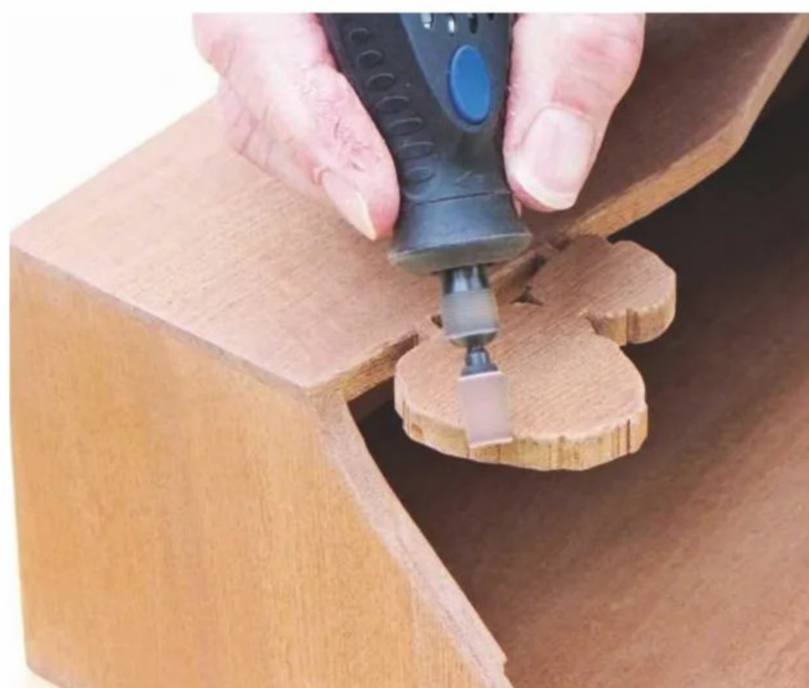
17 Soften the sawn outlines using a multi-tool fitted with a fine grit sanding drum
