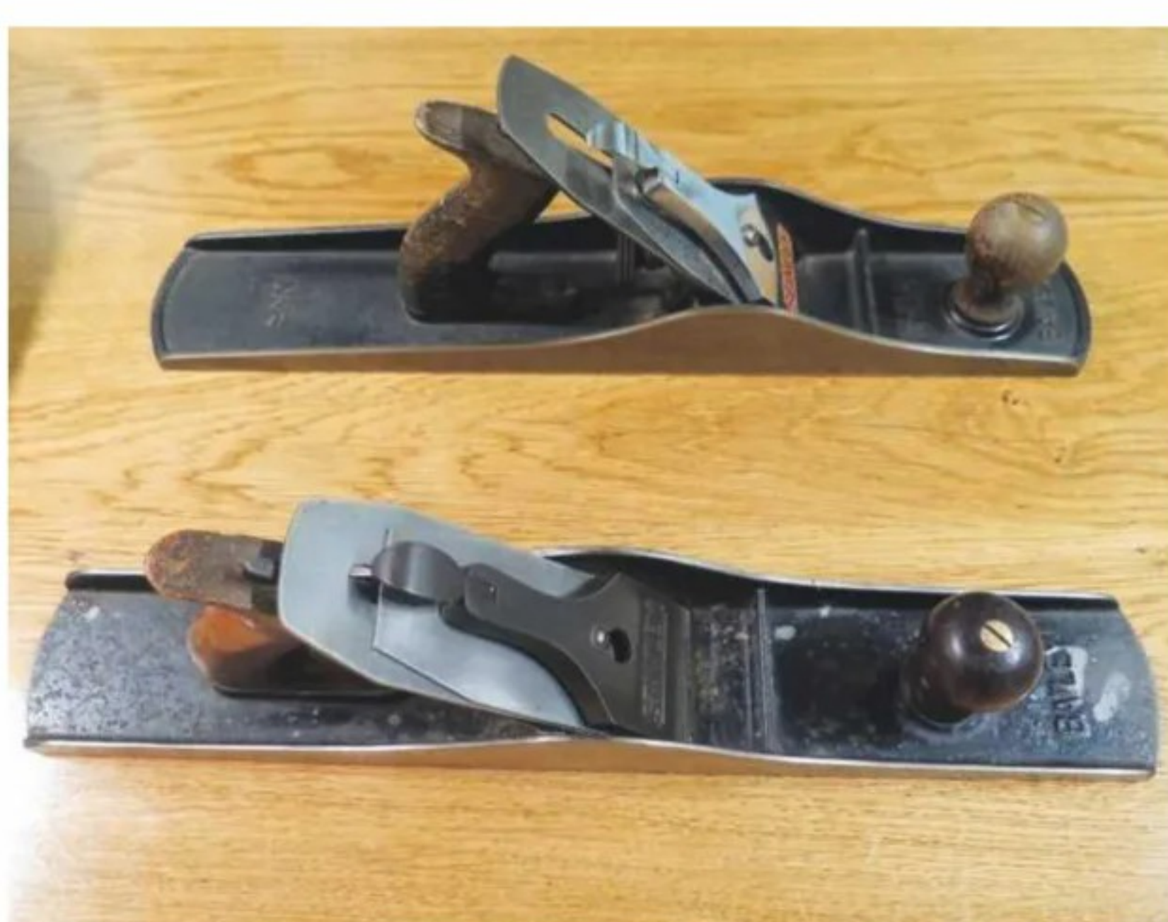
10 The cut down No.7 Stanley plane compared to a standard No.6 – notice the difference in proportions
