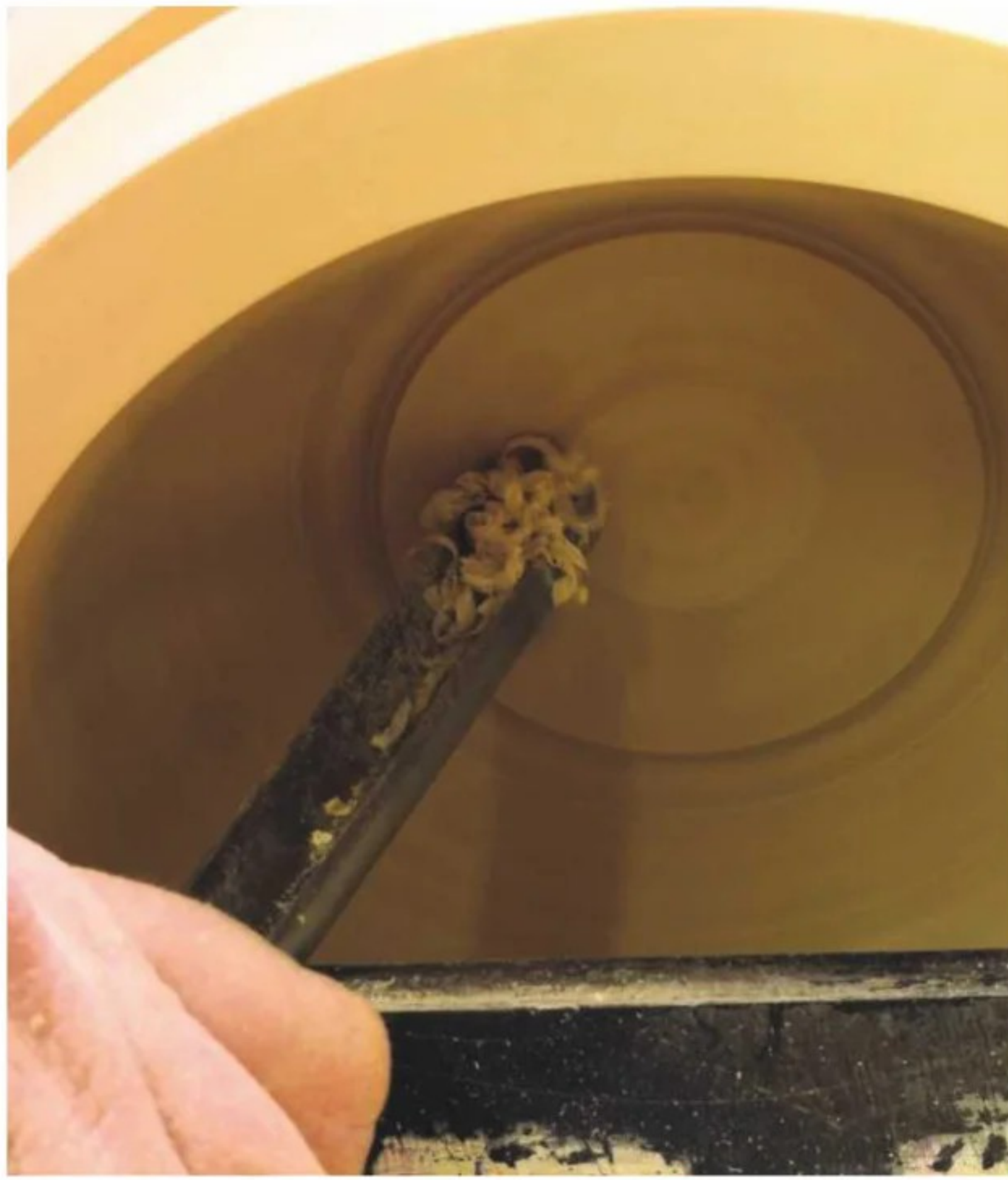
17 The 60° tool is used to cut across the bottom. With this particular gouge, it's easier to rub the bevel owing to the small size
