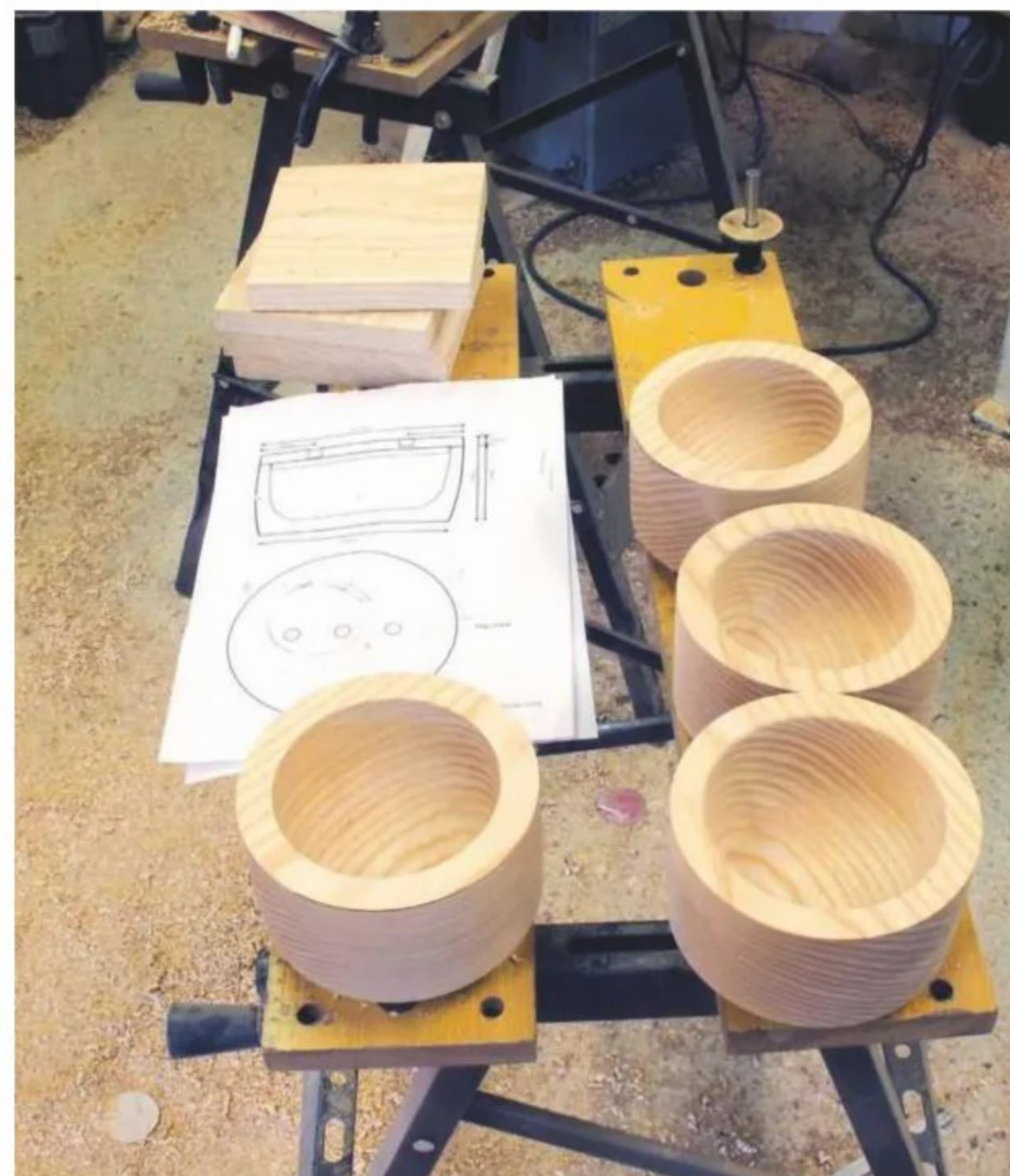
24 The lidded bowls are part-turned to allow for some movement to occur. If time permits, leave for a couple of weeks
