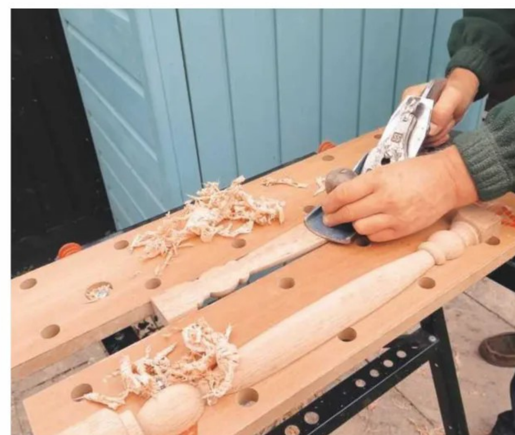
5 Planing the split turning while held in place on a portable workbench...
