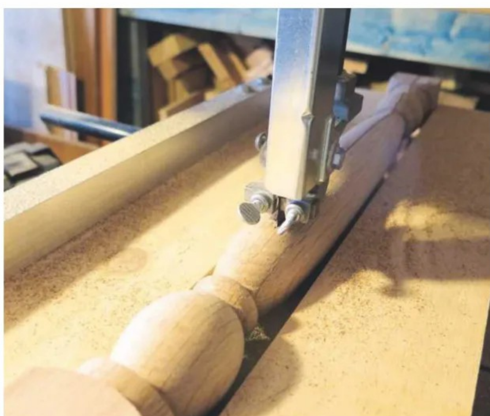
4 Using a bandsaw to split the turning
