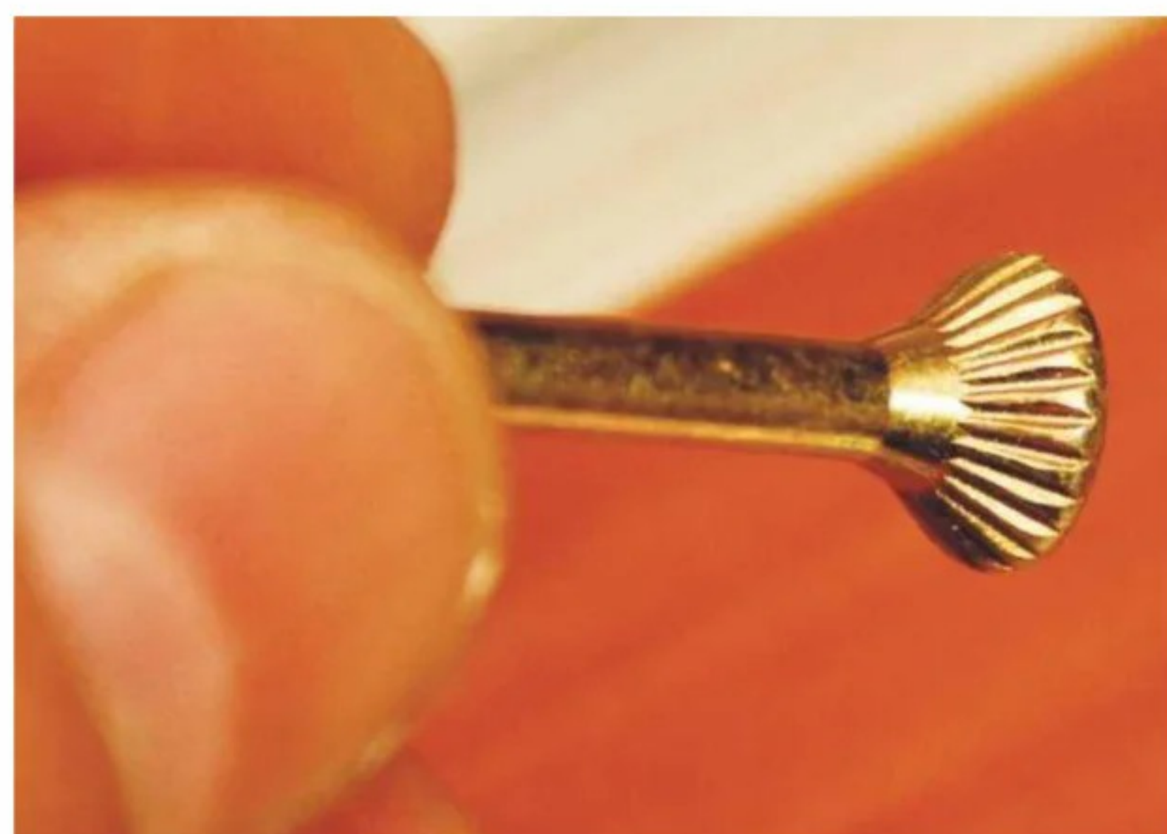
These grooves work to remove waste, which allows for clean countersinking
