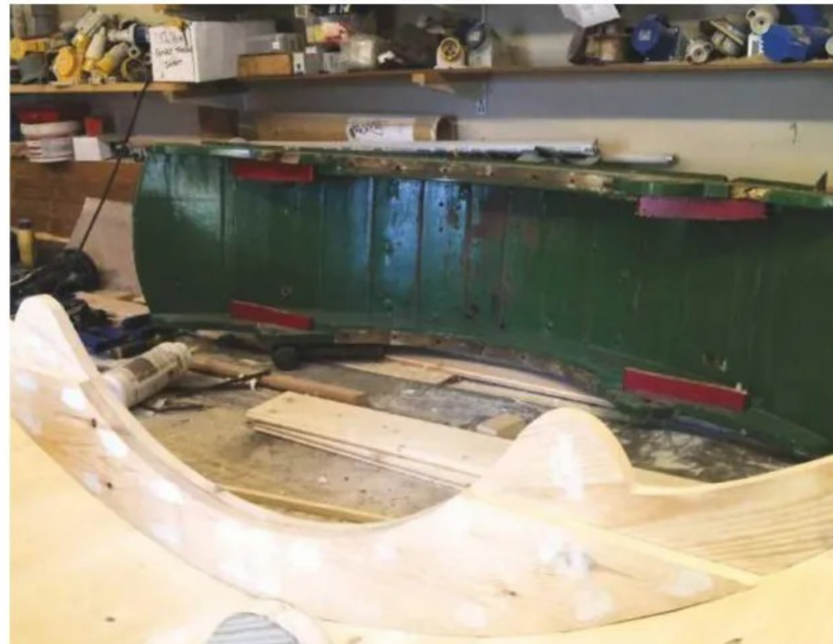
Constant wear and tear means that some rides, such as this swing boat, have to be made anew
