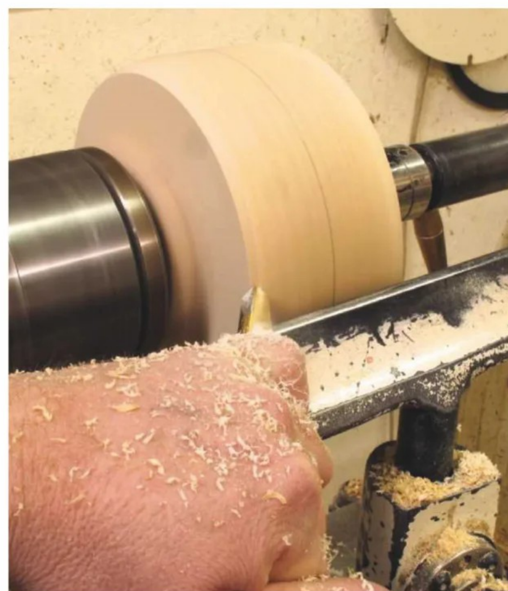
10 Care needs to be taken with this cut as you're working a little cack-handed when rounding over the bowl's underside. Alternatively, this step can also be carried out from the initial fixing
