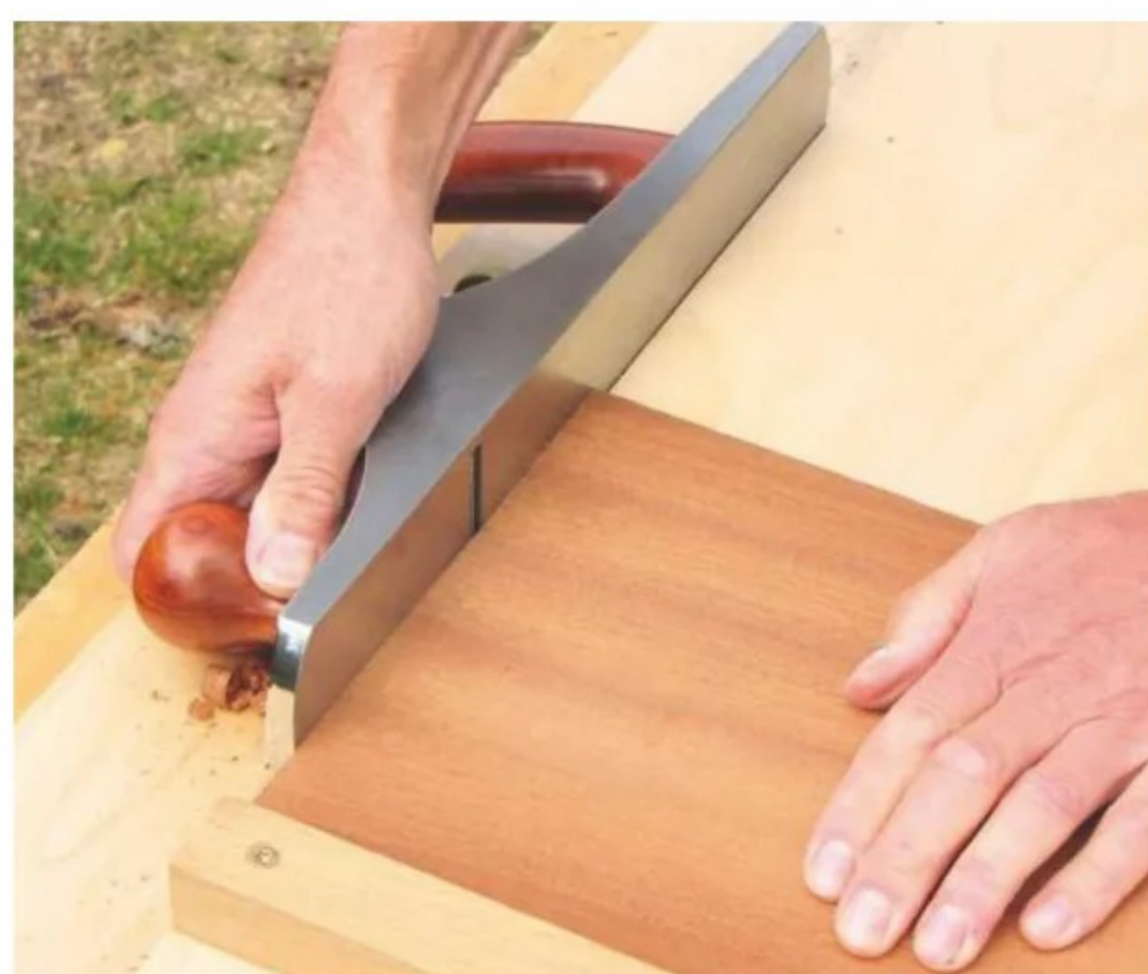
2 Using a shooting board, plane the bottom edge of all four panels, plus the divider. Trim ends square
