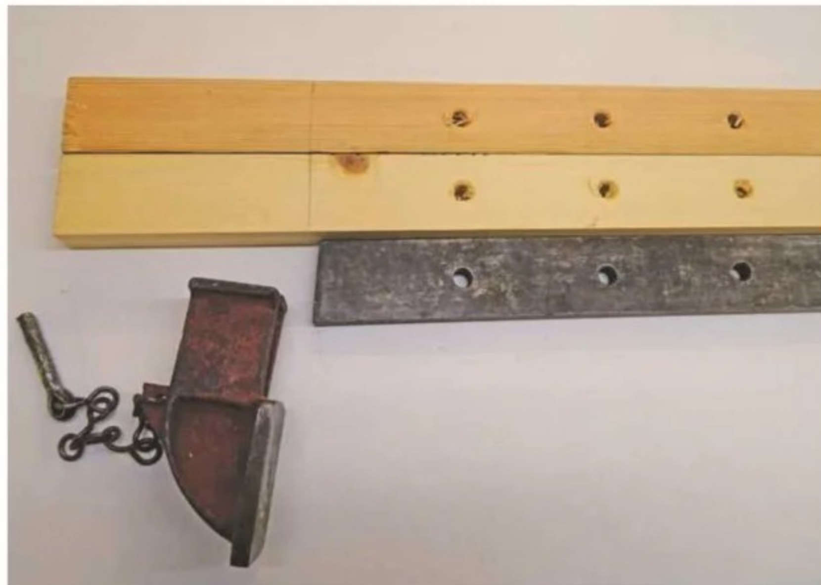
7 Two wooden pieces drilled to match holes in the cramp shaft
