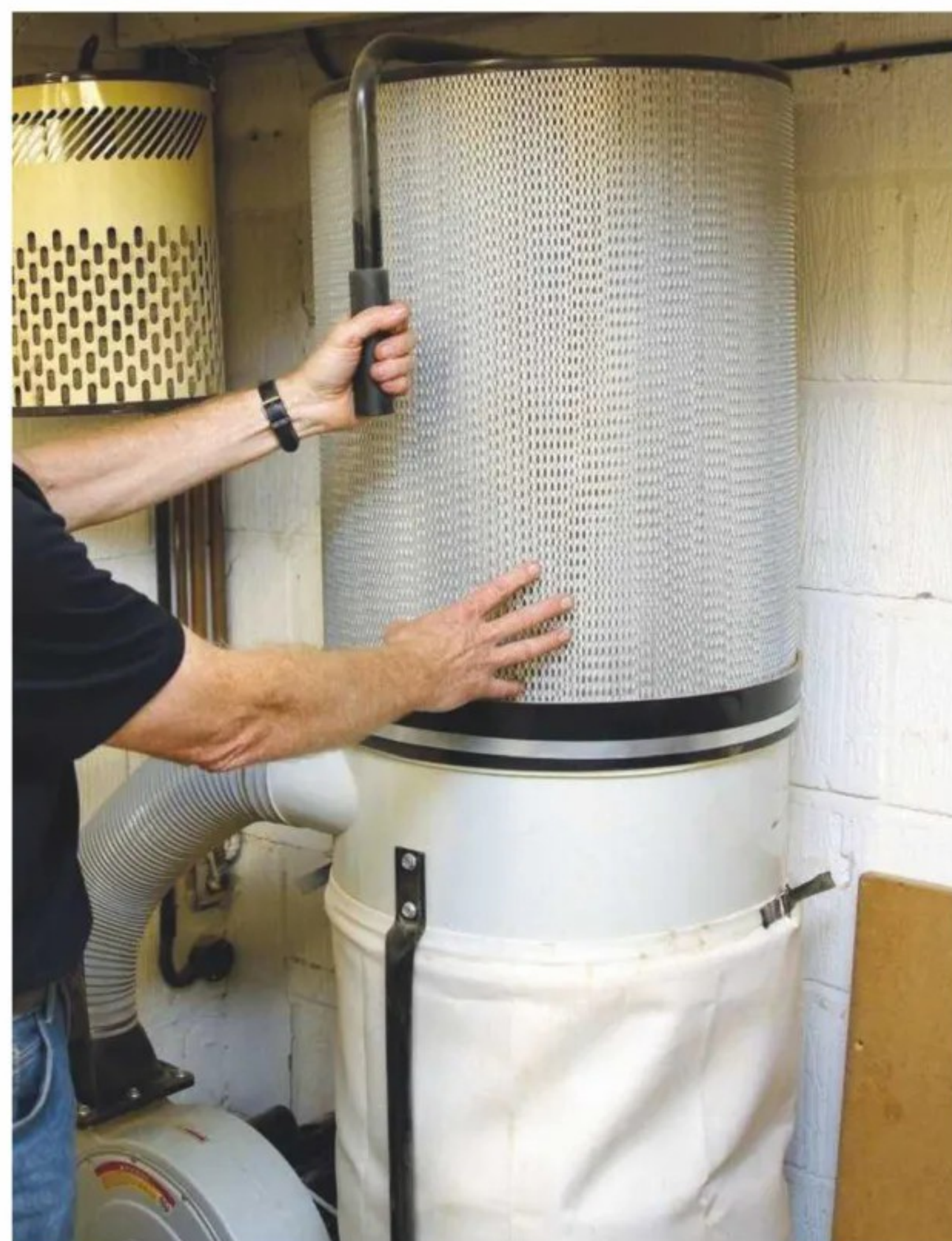
12 A high efficiency particulate air filter has many folds, which increases surface area, and a hand-operated paddle shakes dust off the inside
