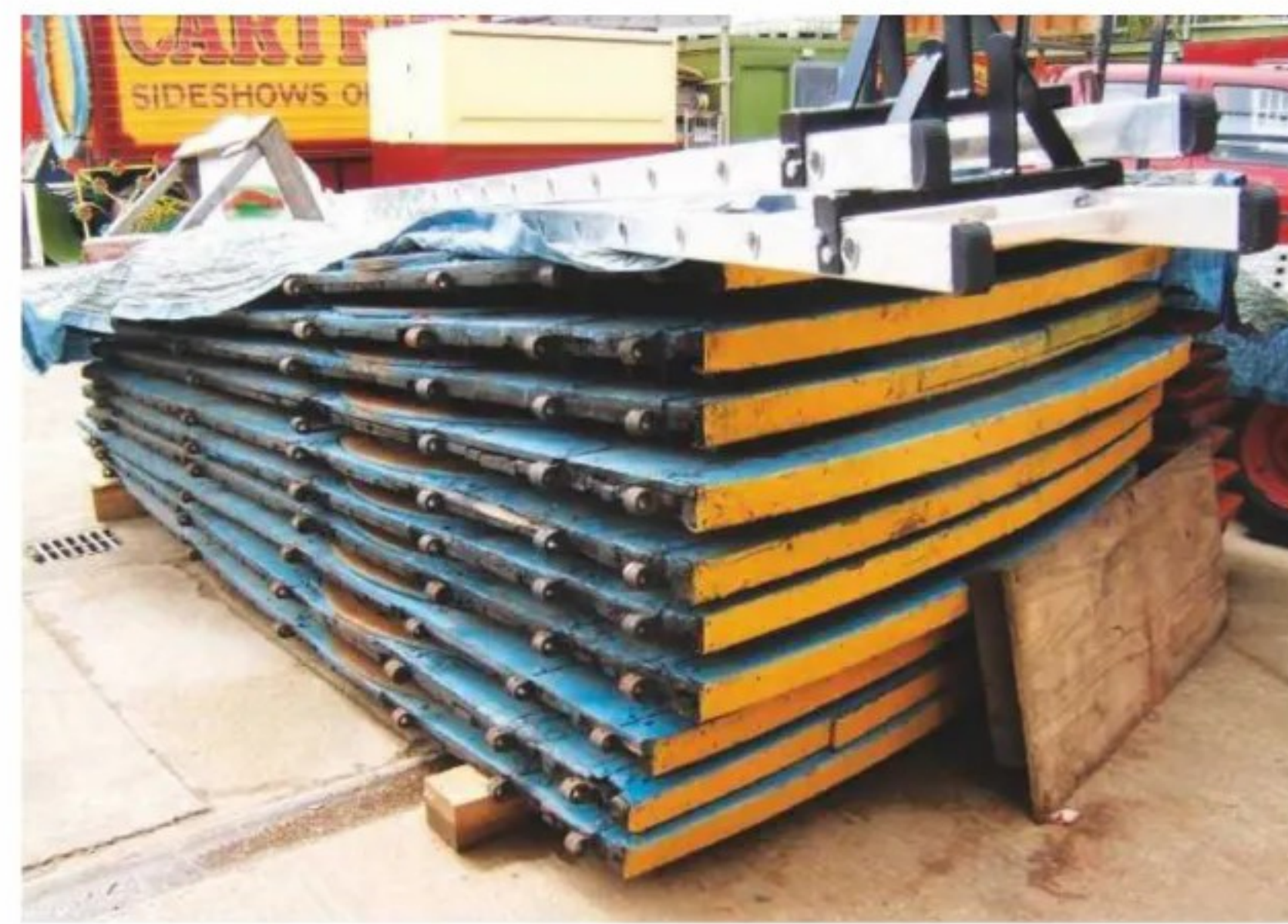
These wedge-shaped boards are taken from the floor of a waltzer
