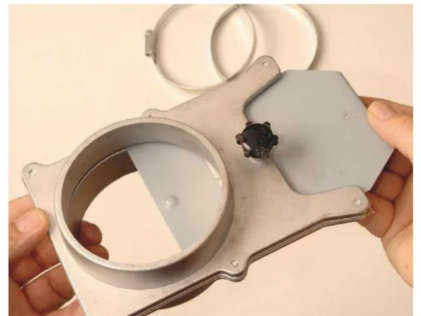
8 Blast gates are sliding valves in extract systems, fitted to keep the airflow where it's needed at full speed
