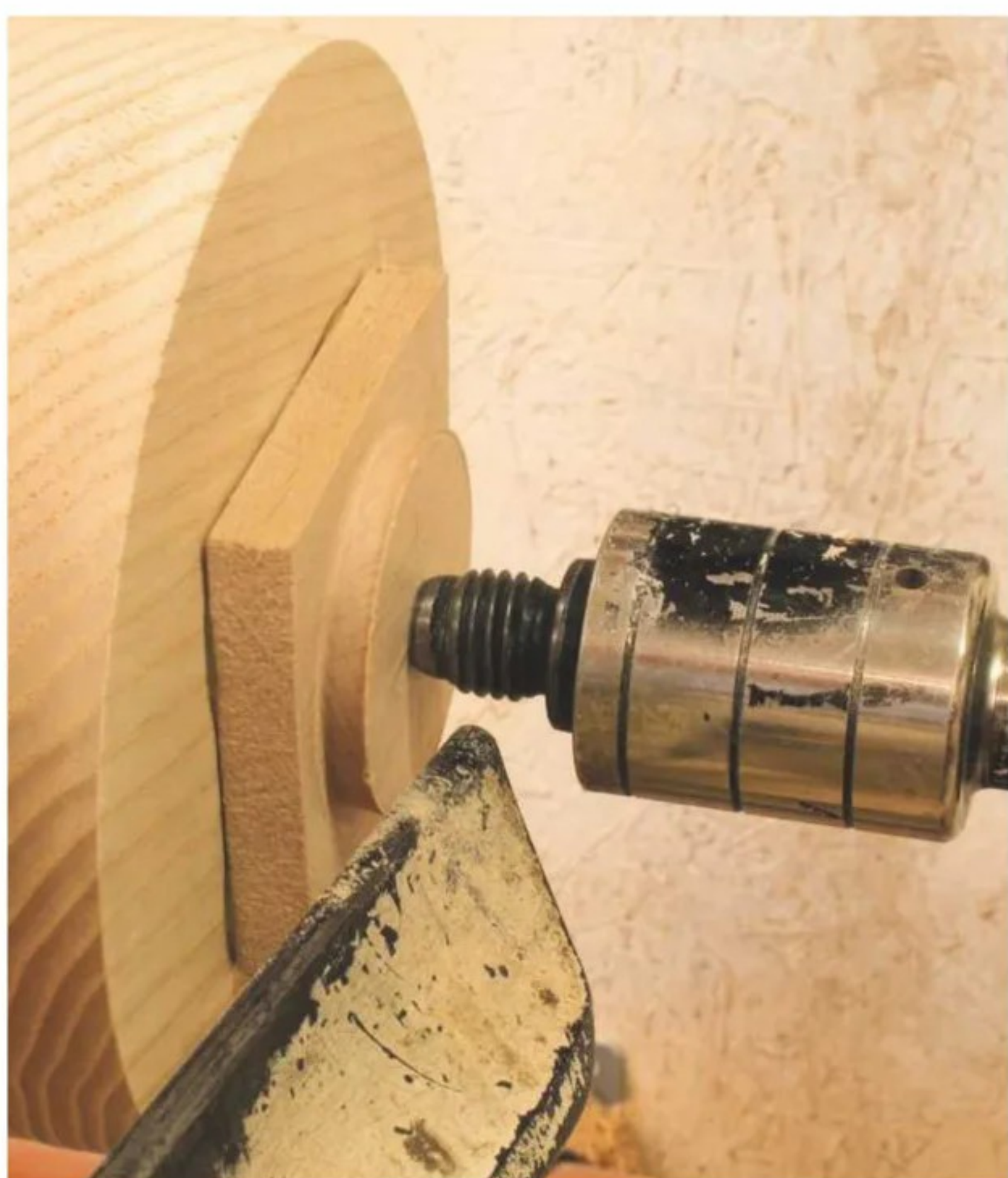
8 Cut a spigot on a scrap offcut, so that it suits your chuck. A dense timber such as beech is ideal, but MDF is best avoided due to its inherent weakness
