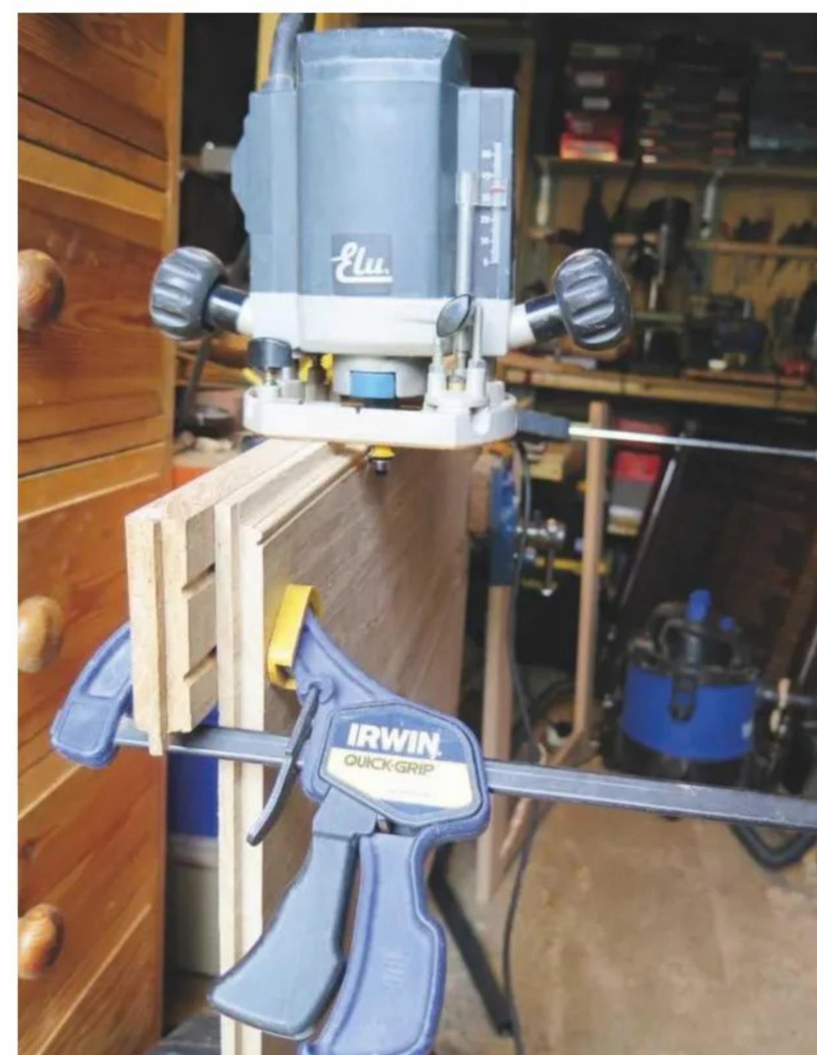
11 Carefully routing a corner bead on one of the rebated edges
