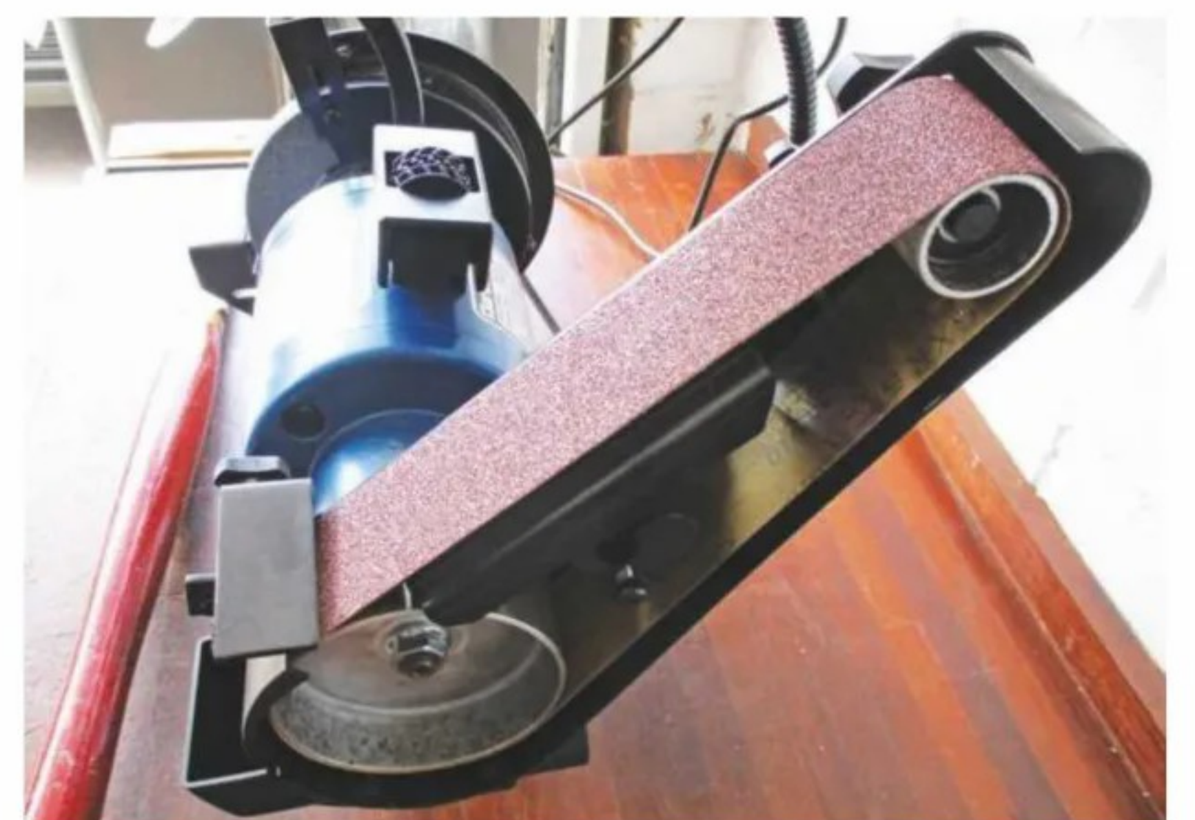
Good access for belt replacement or maintenance
