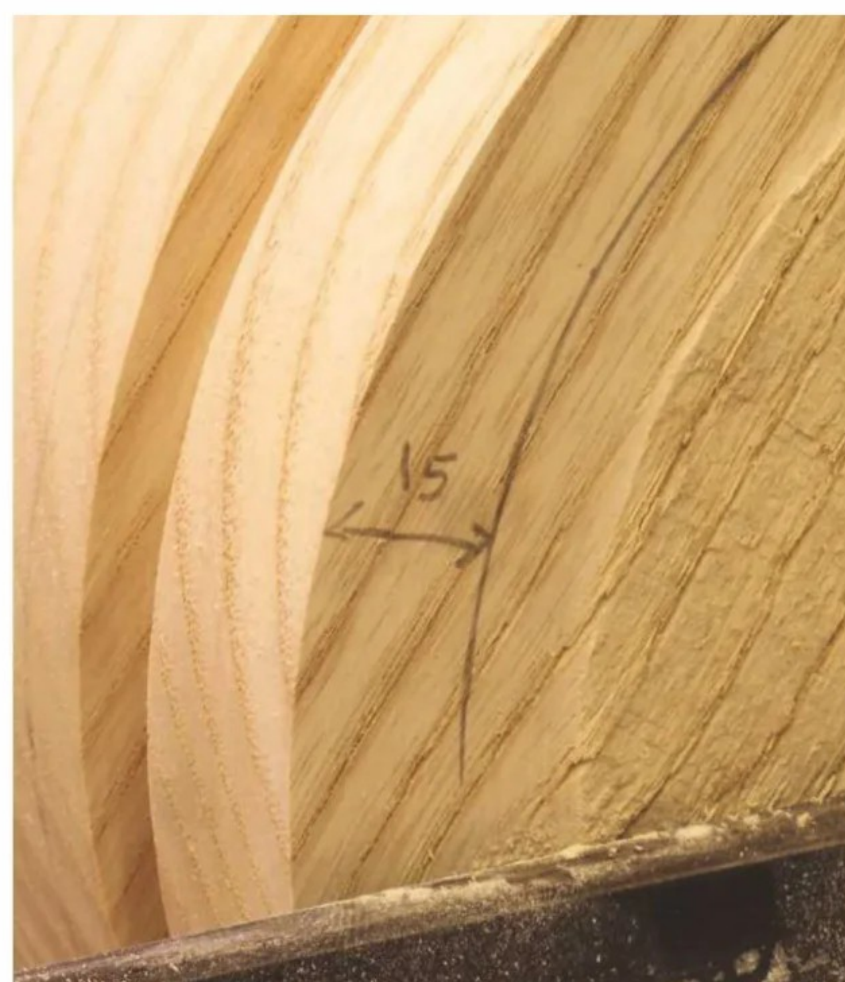
13 This particular design has a 15mm thick rim, which needs to be marked using a pencil. If you're worried about the tool skating across the surface when starting the cut, make an incision with a parting tool
