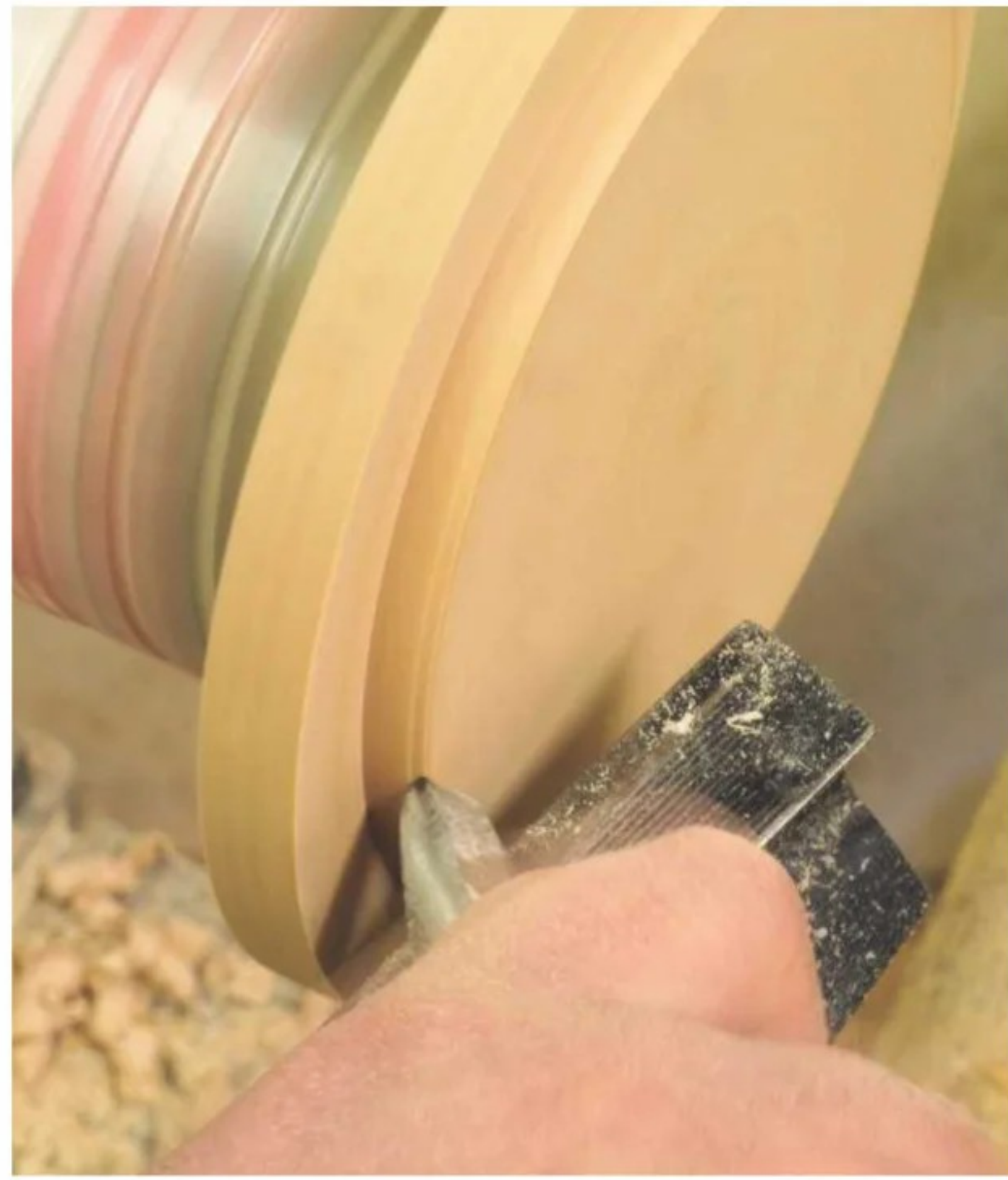
27 A light pass with a spindle gouge ensures a good finish on the spigot – one which requires little or no sanding
