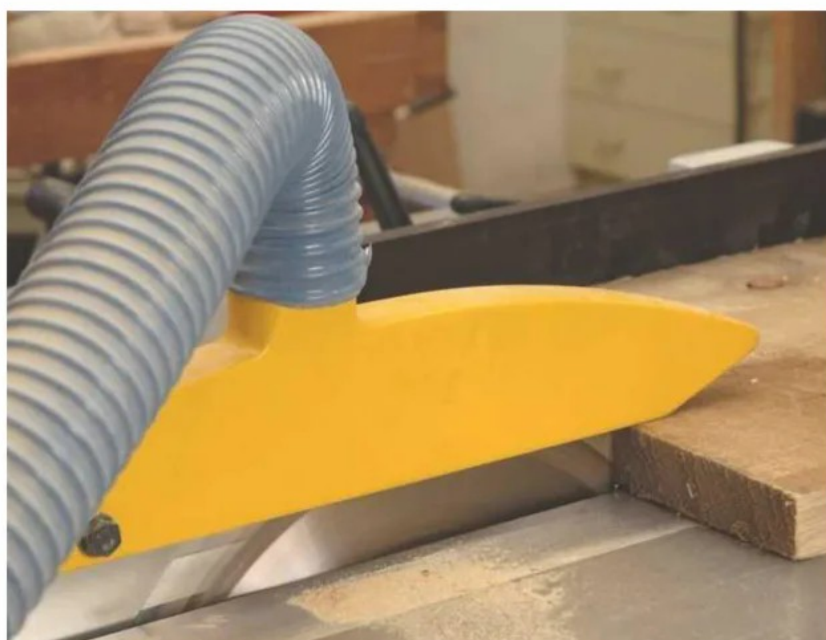
2 The table saw produces a fast stream of dust-laden air, which is then collected by the crown guard
