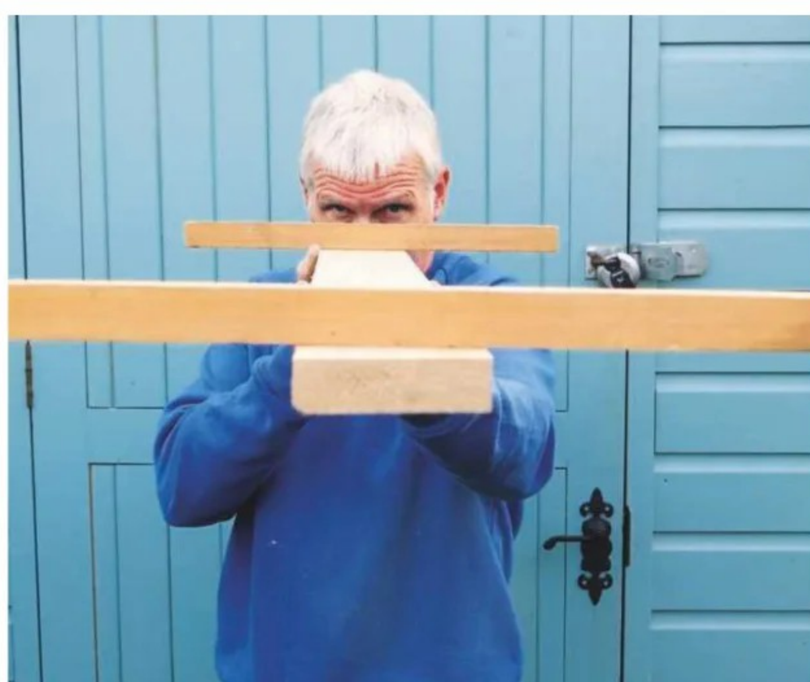
7 Checking the oak board for wind before running through a thicknesser...
