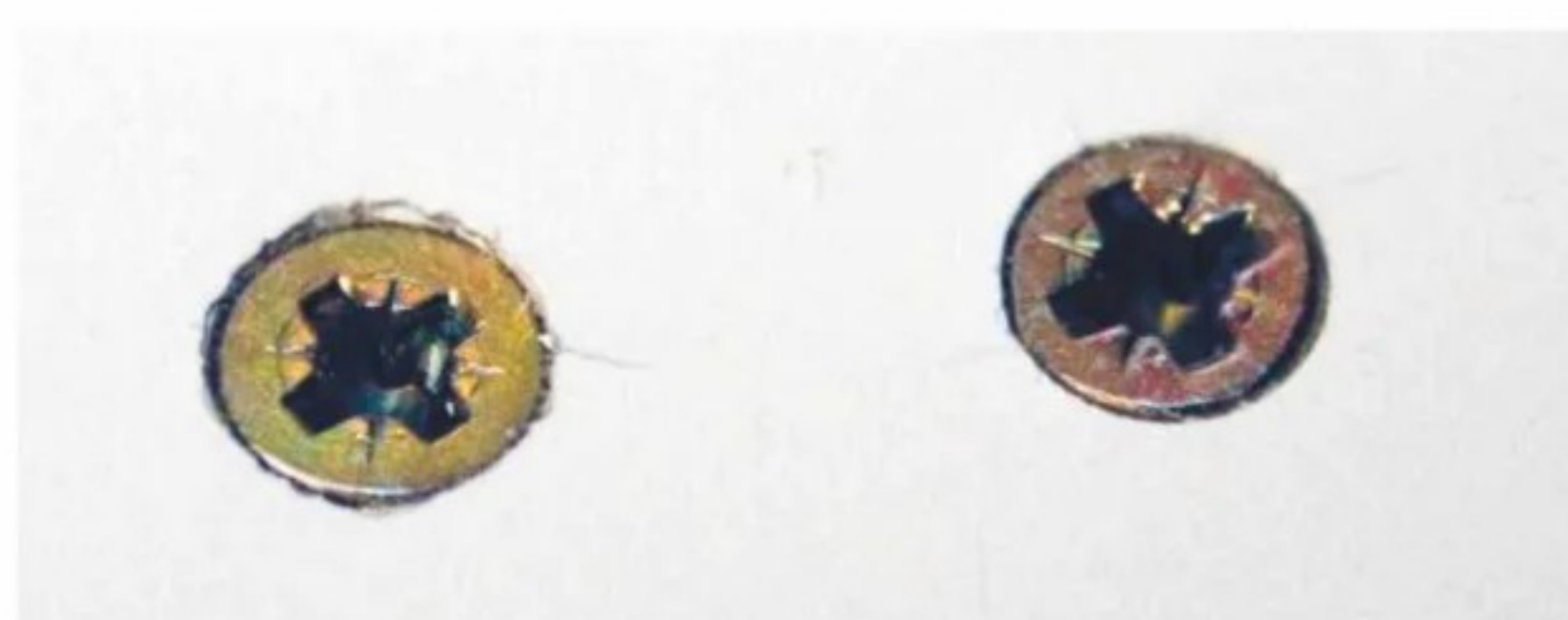
The rival screw on the left shows crushing around the head's perimeter
