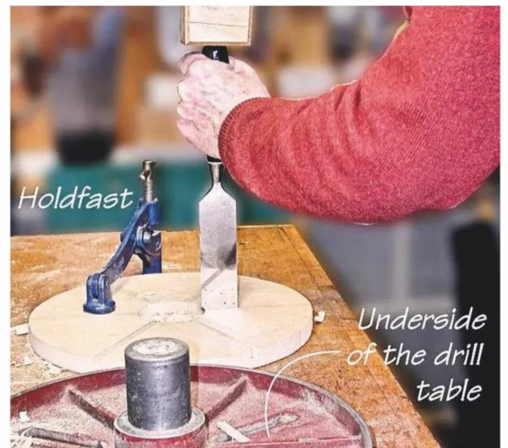
7 I use a wide chisel to cut a groove's boundaries
