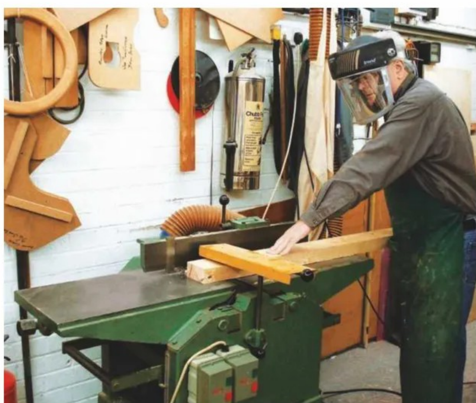
1 Planing a reference face and edge before thickening the stiles
