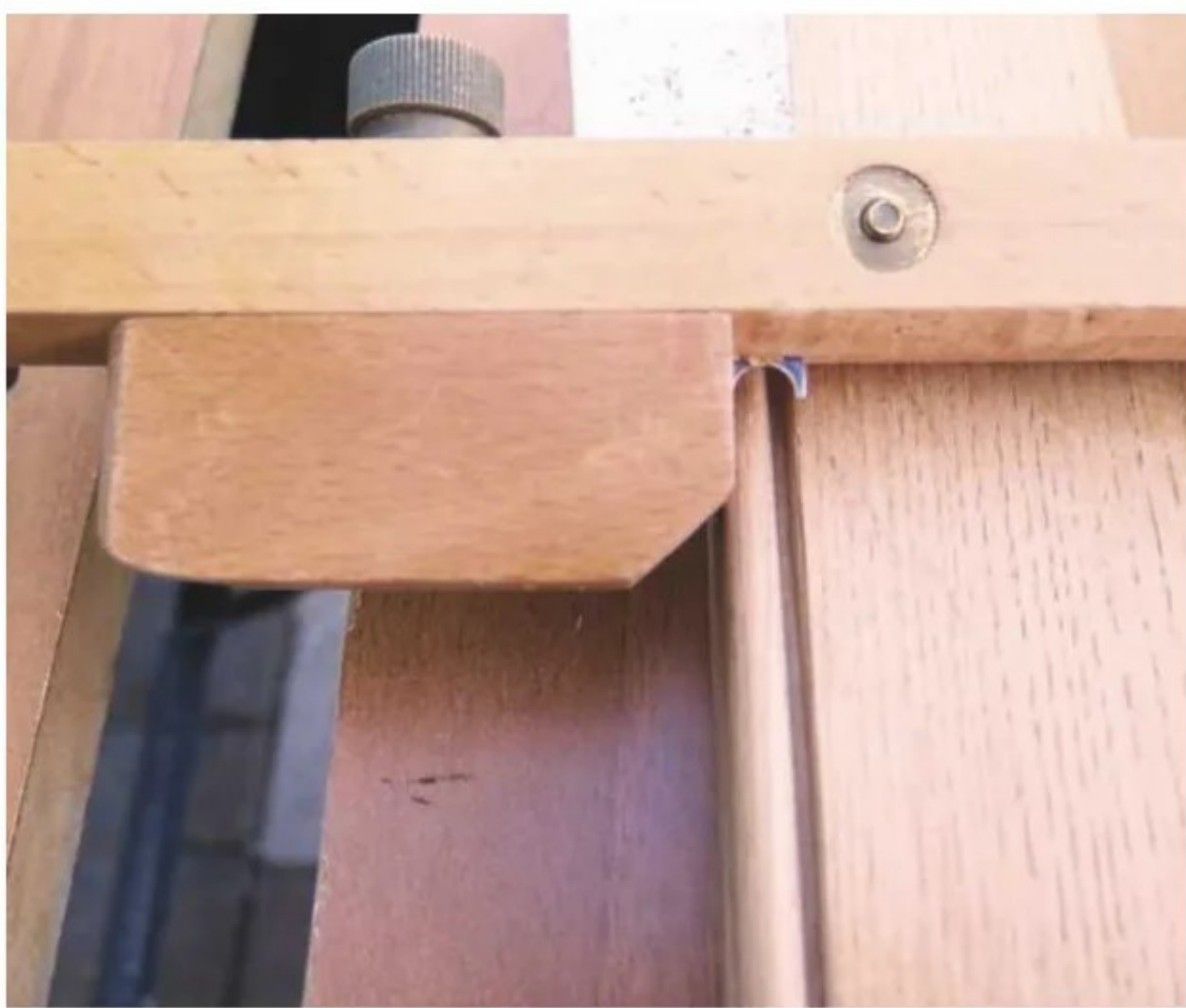
12 Homemade cutter in scratchstock
