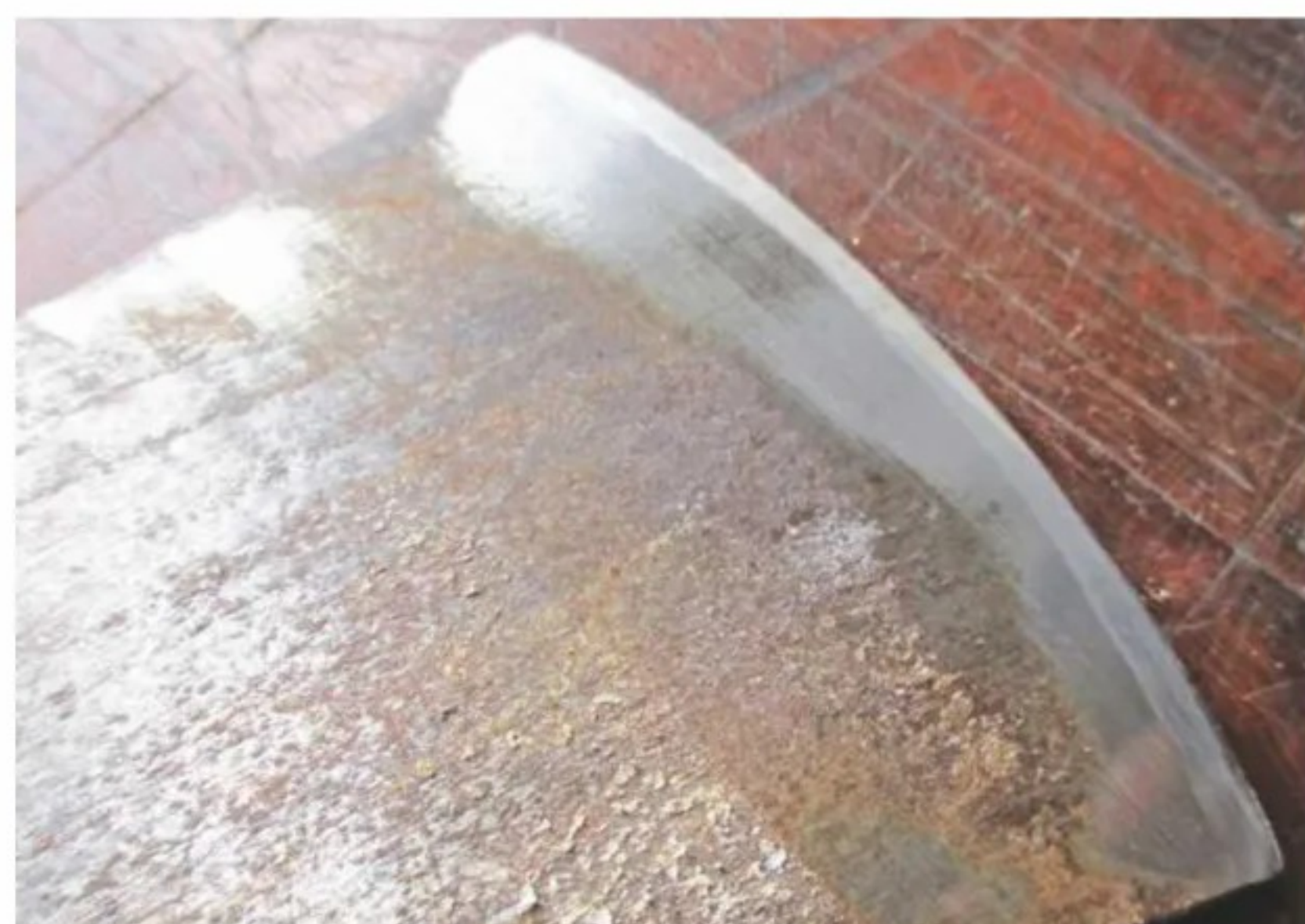
Good results are achieved using a coarse belt
