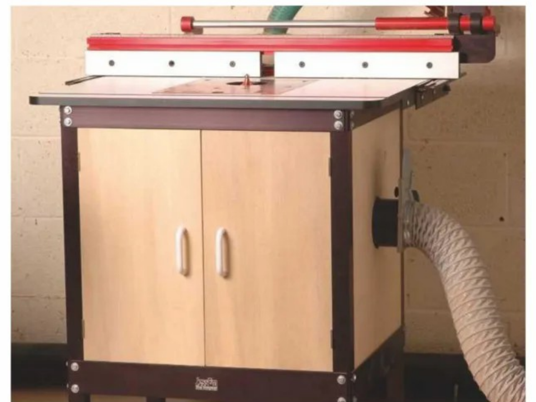
6 A router mounted in a router table contains much of the dust produced
