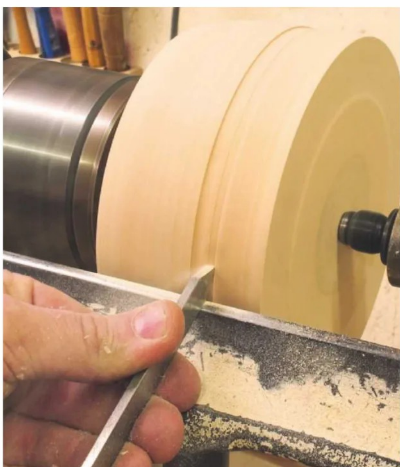
11 This particular design has a groove to accept the rope; use a freshly-sharpened parting tool with light cuts. If carried out prior to hollowing, you'll end up experiencing less vibration
