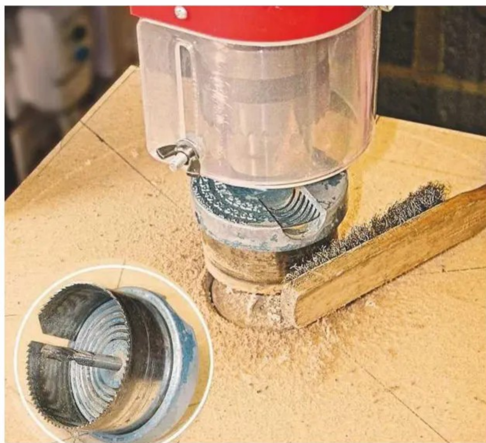
5 In order to clean the clogged-up teeth, I use a well-worn brush
