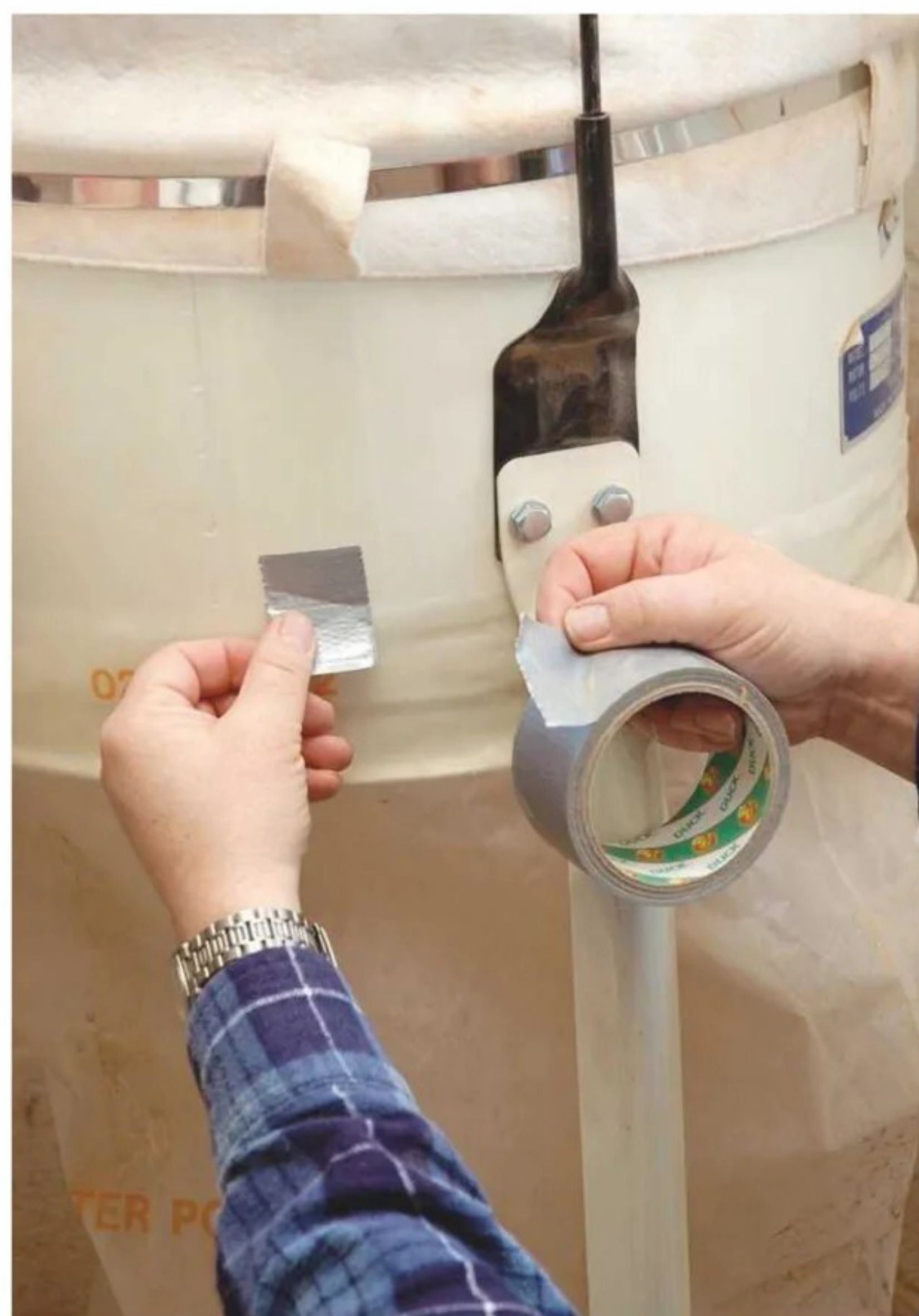
14 Strips of duct tape provide a temporary fix to hold a new sack in place while clips are fitted, which helps to get around the 'not enough hands' problem
