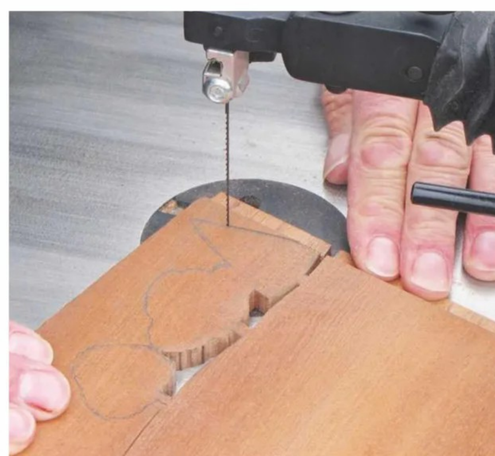
9 Drill holes for inserting the blade where necessary. Using a scrollsaw, carefully follow the pencil line
