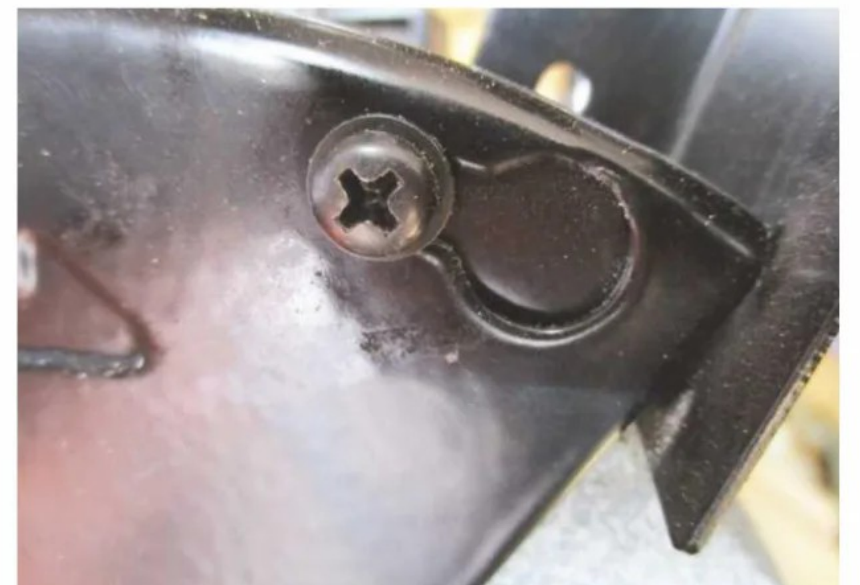
Keyholes facilitate quick removal of the wheel cover
