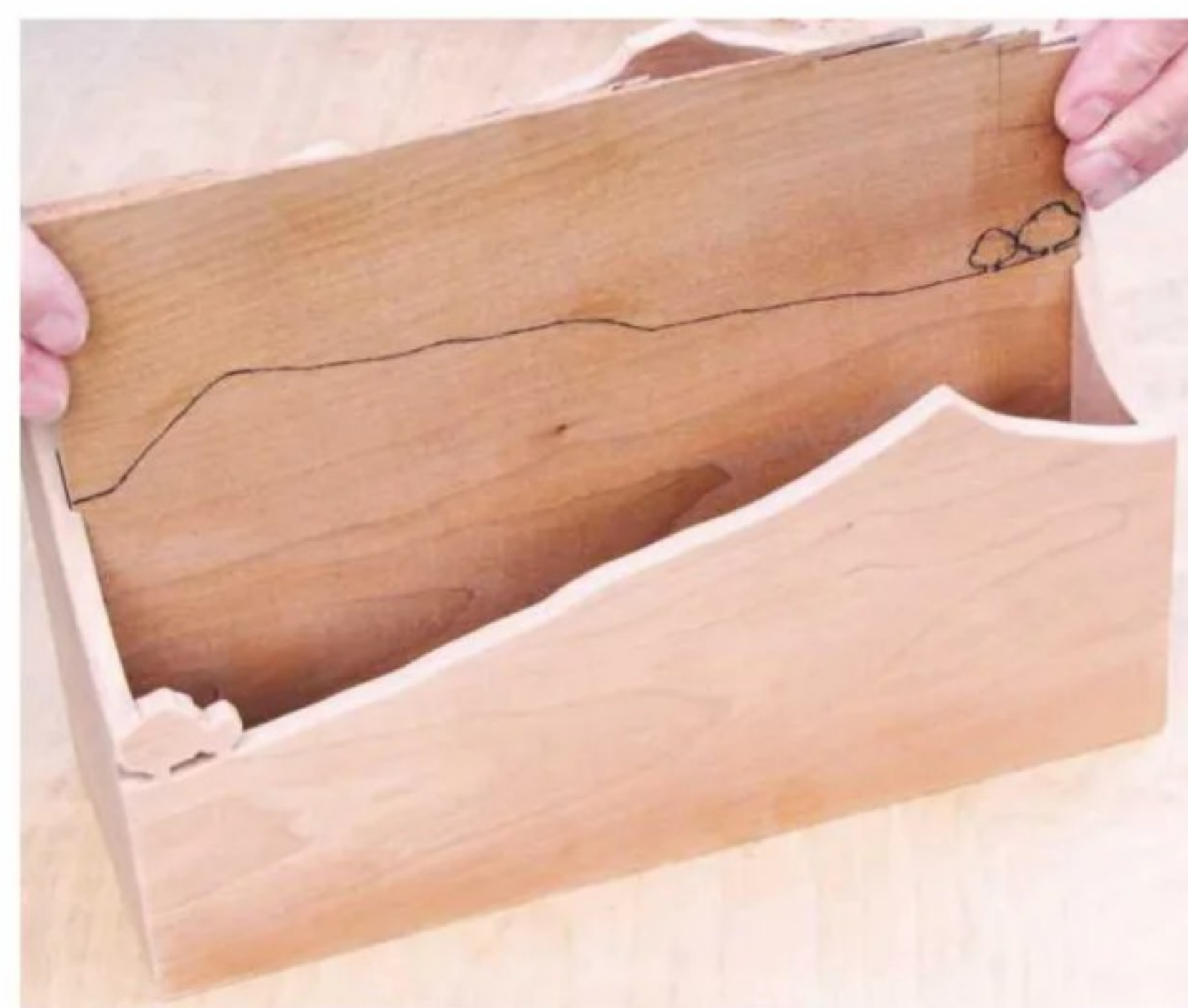
18 Cut the divider so that it slides between the grooves. Saw the outline, then sand
