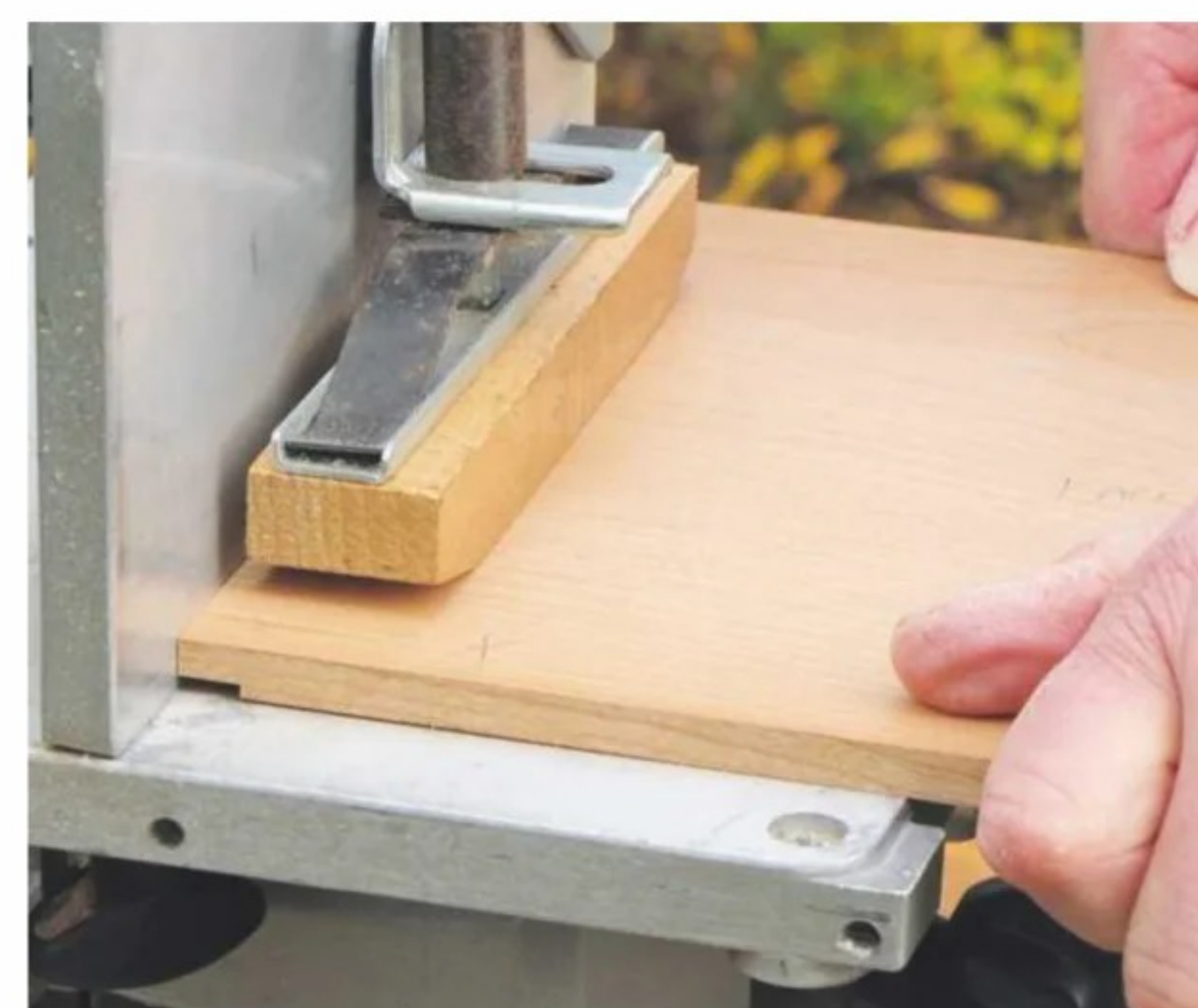
3 Mark out ends of front and back panels. Using a router table, form rebates to half the timber's depth
