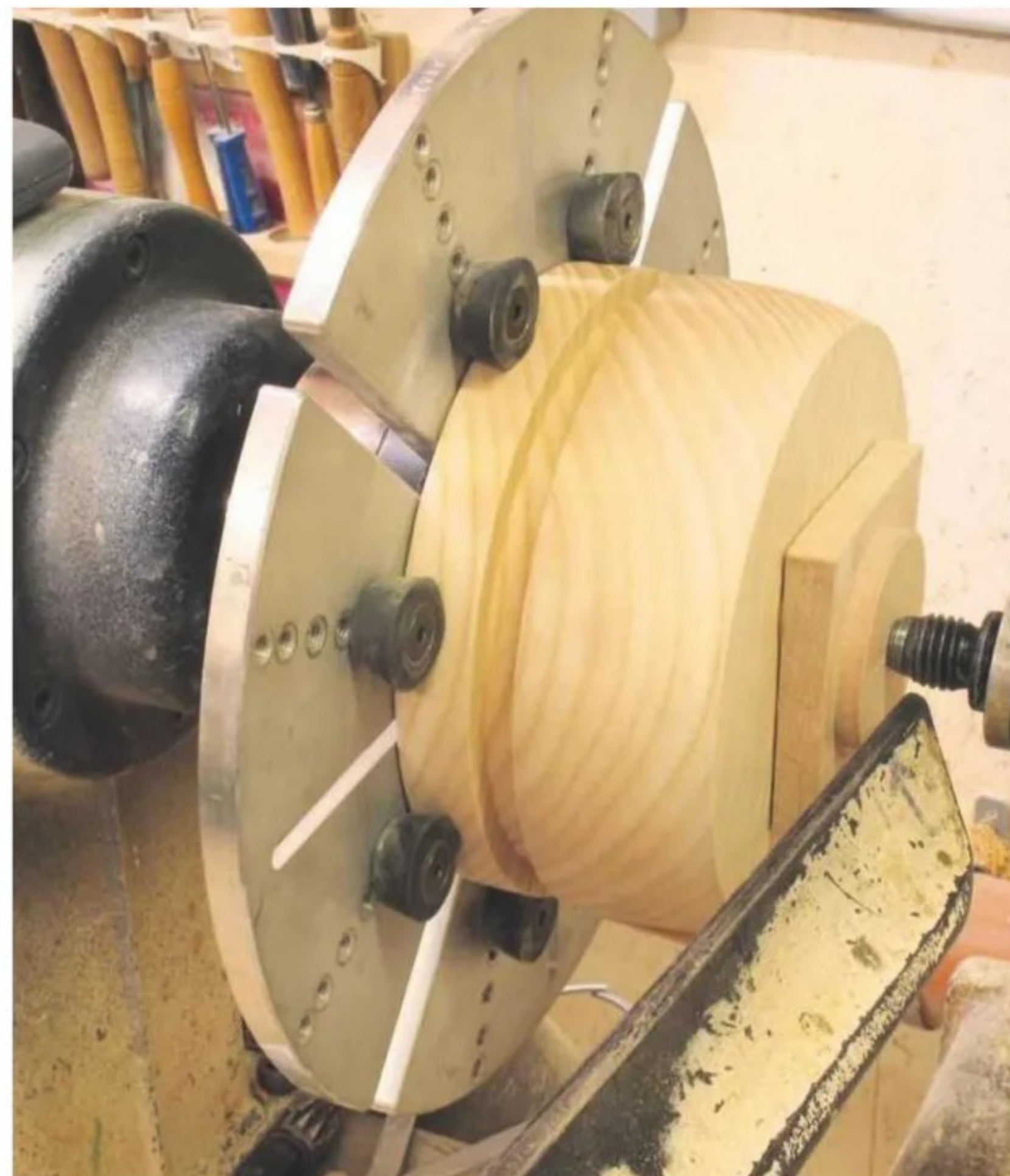
21 A set of plate jaws is suitable for re-chucking the bowl, allowing me to clean off the beech block attached to the bottom. For safety reasons, adhere to the maximum speed printed on the jaw sides
