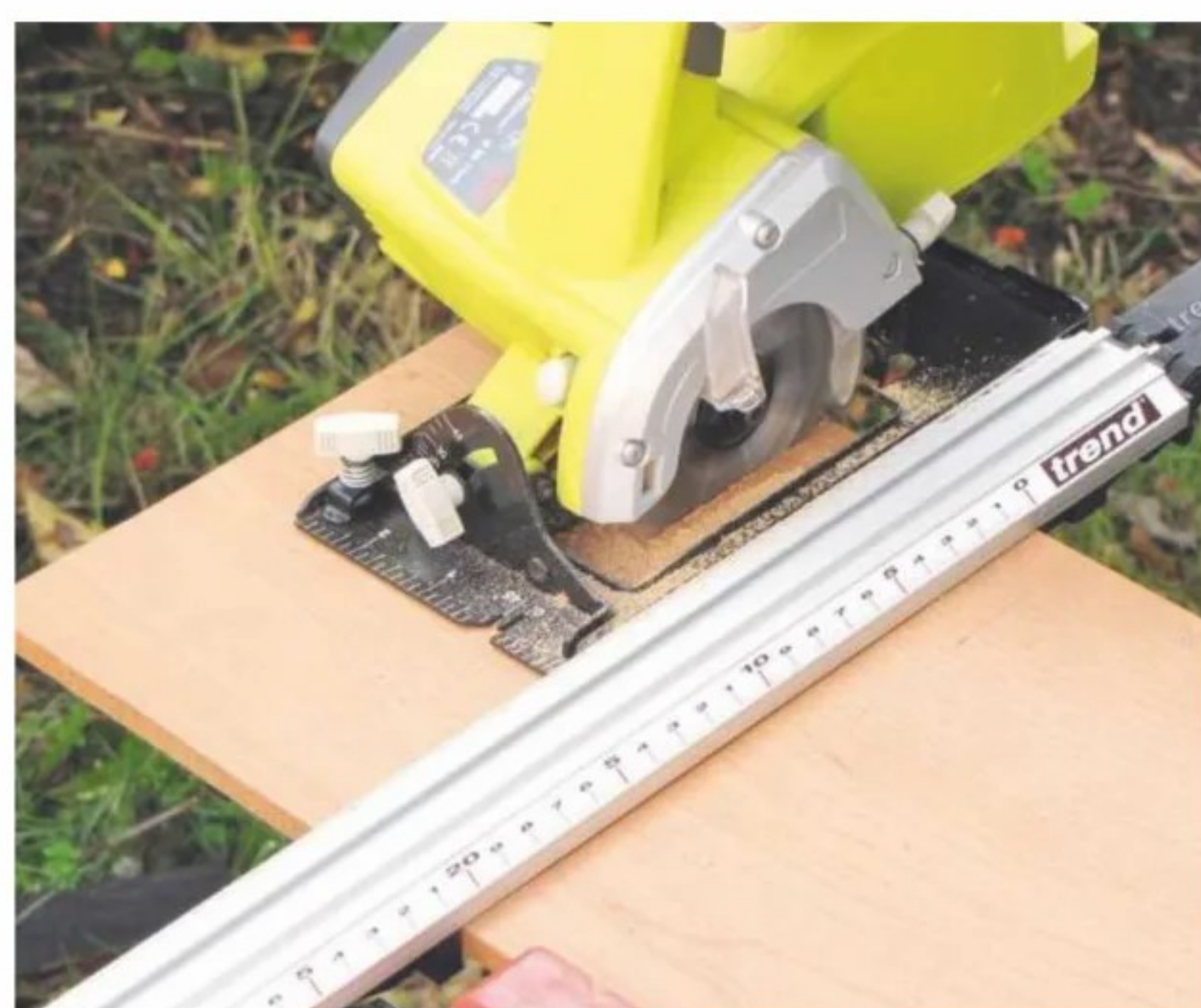
1 Thickness timber to around 8mm and saw panels to length. Cut the front and back 2mm oversize
