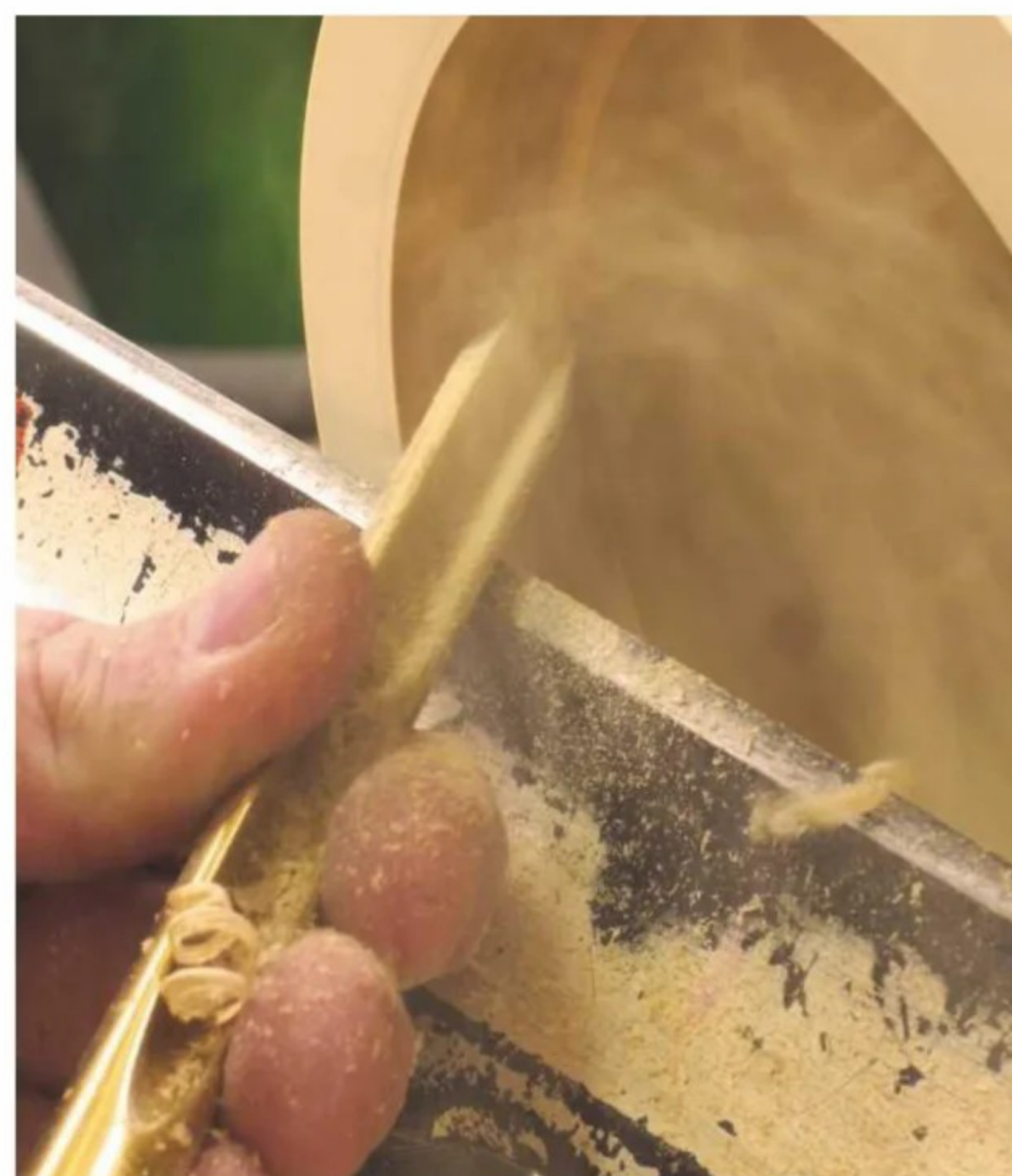
16 Advance the tool into the work, keeping the bevel in constant contact, which will avoid experiencing a catch
