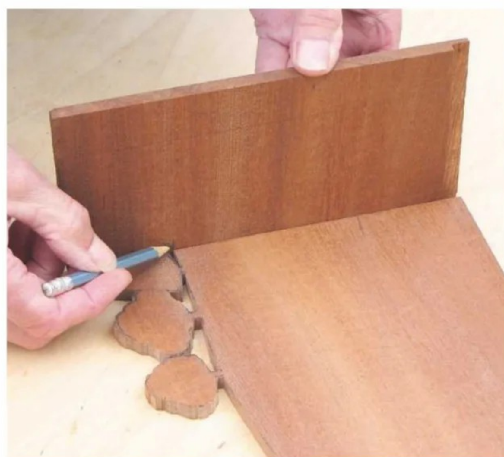
10 With outlines cut on the front and back panels, mark the height on both end sections
