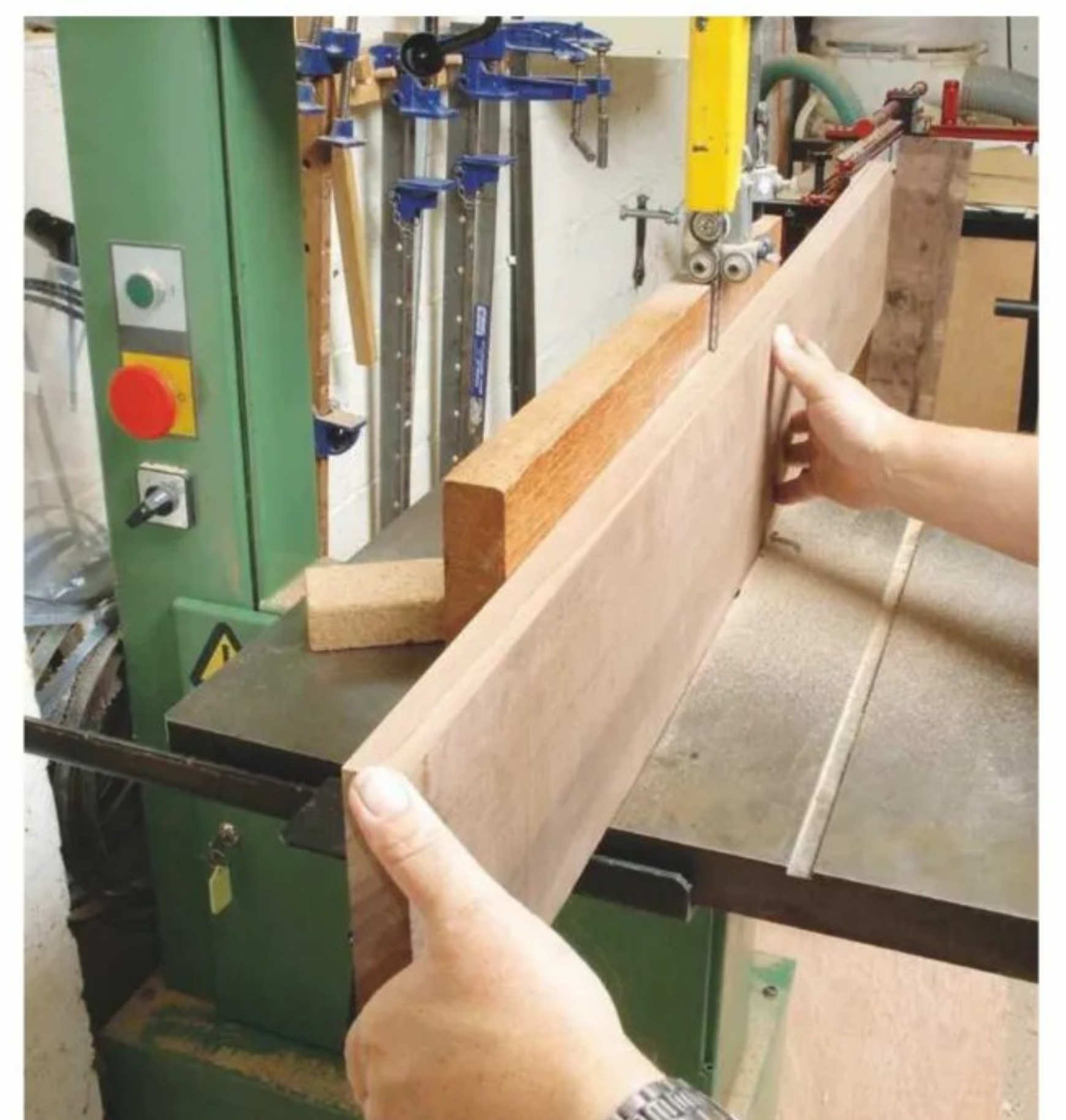
4 When a bandsaw is used to rip through timber edgewise, it cuts a considerable depth and therefore produces a volume of dust
