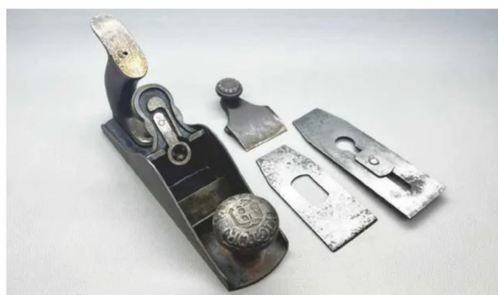
Leonard Bailey No.4 Victor bench plane – an early version where the loop adjuster works off the cap screw instead of a pin-type adjuster – 300 × 200 × 100mm
