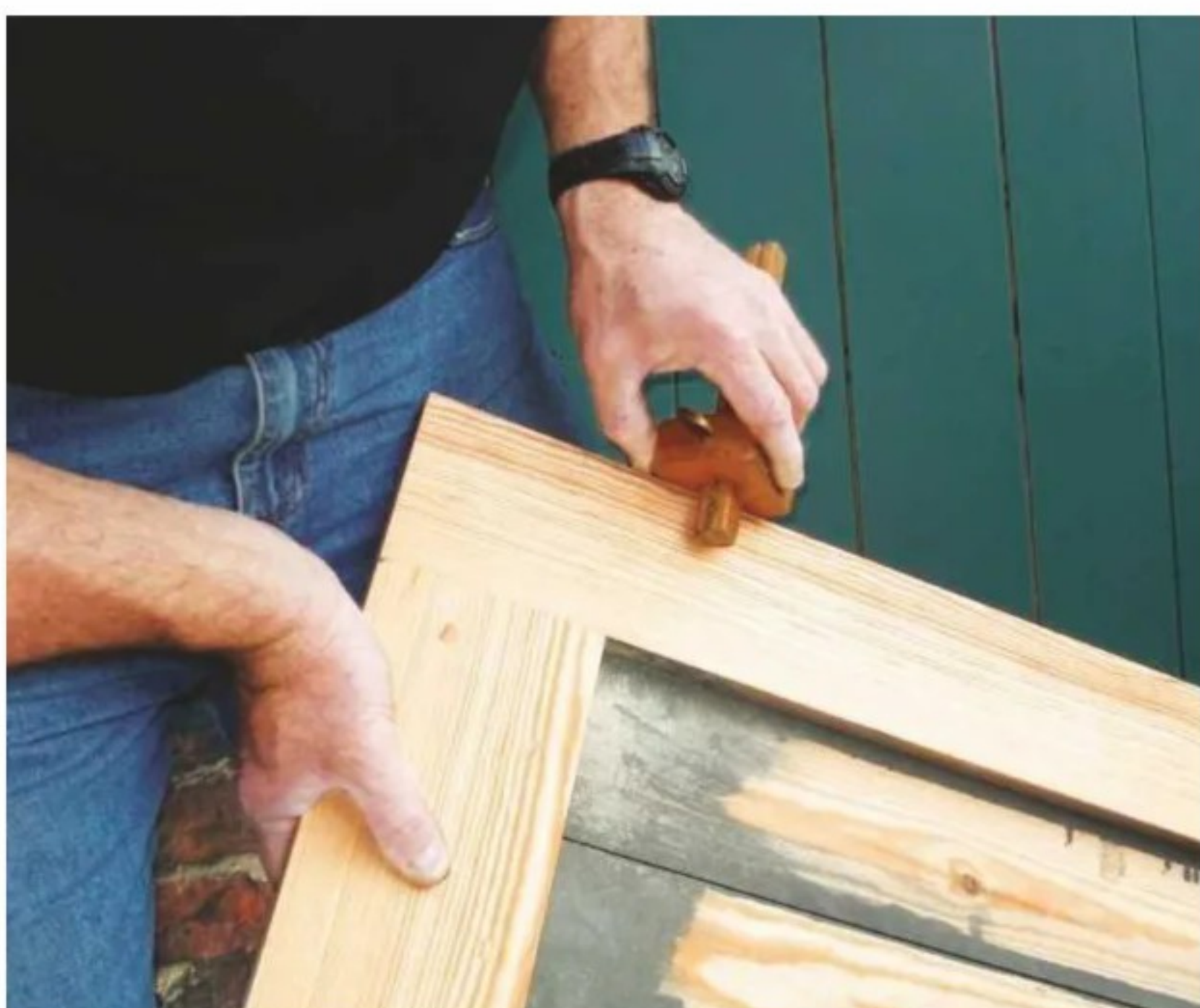
18 To ensure uniformity, use a gauge to mark door rebates
