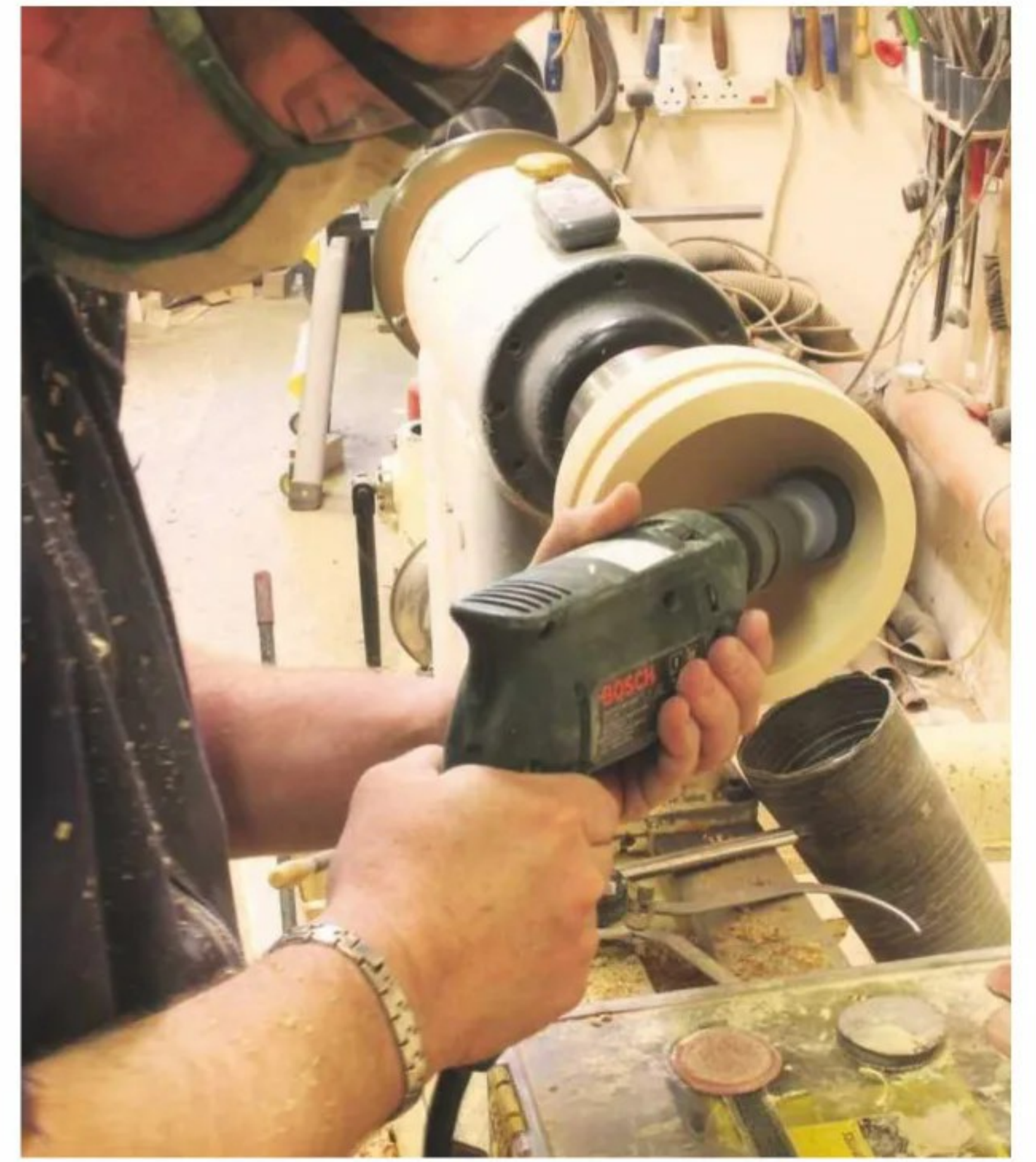
19 To quickly achieve a good finish, traditional power sanding is the most effective method
