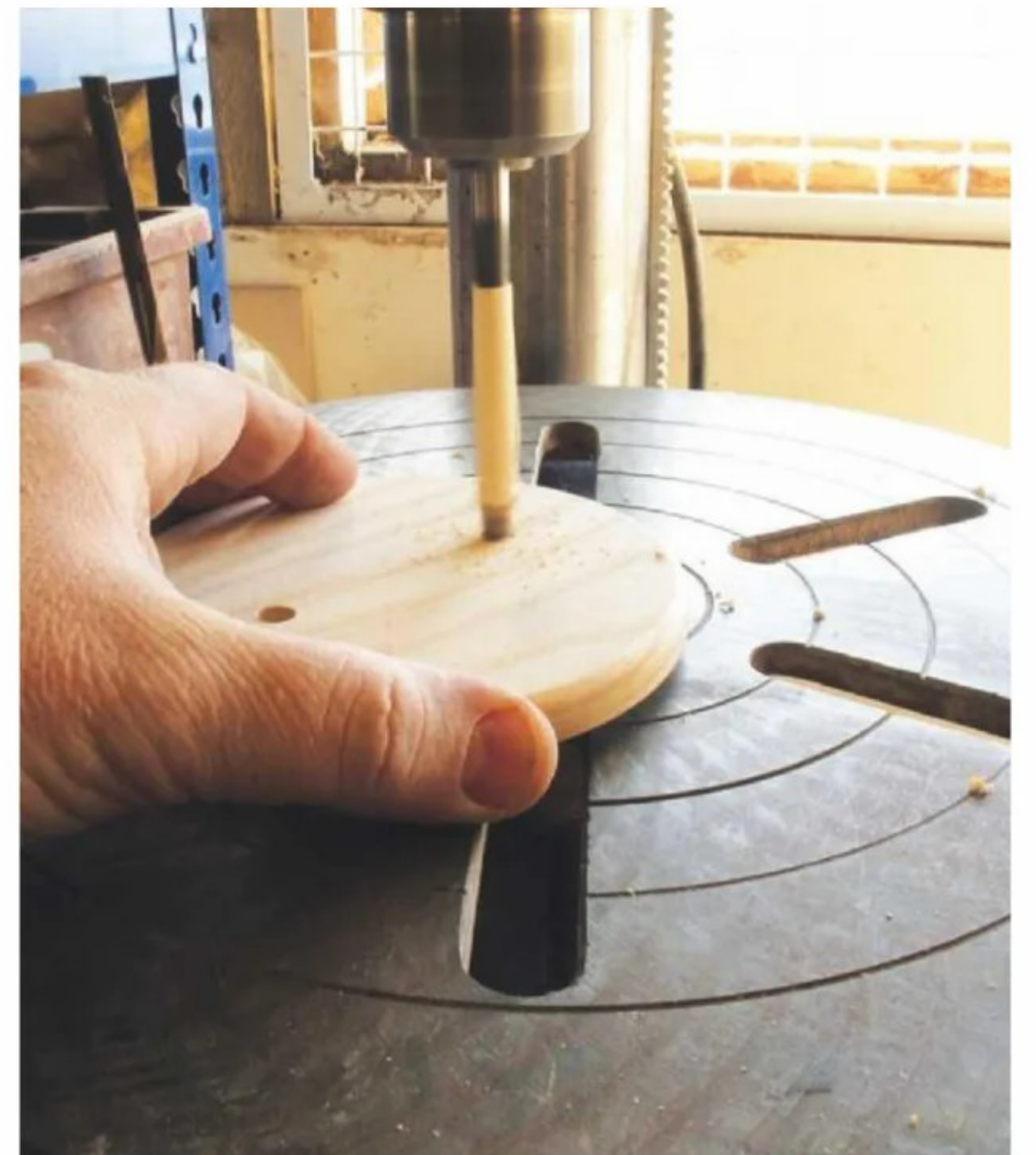
31 According to the plan, one 8mm diameter hole is required for two of the lidded bowls, and two for the others
