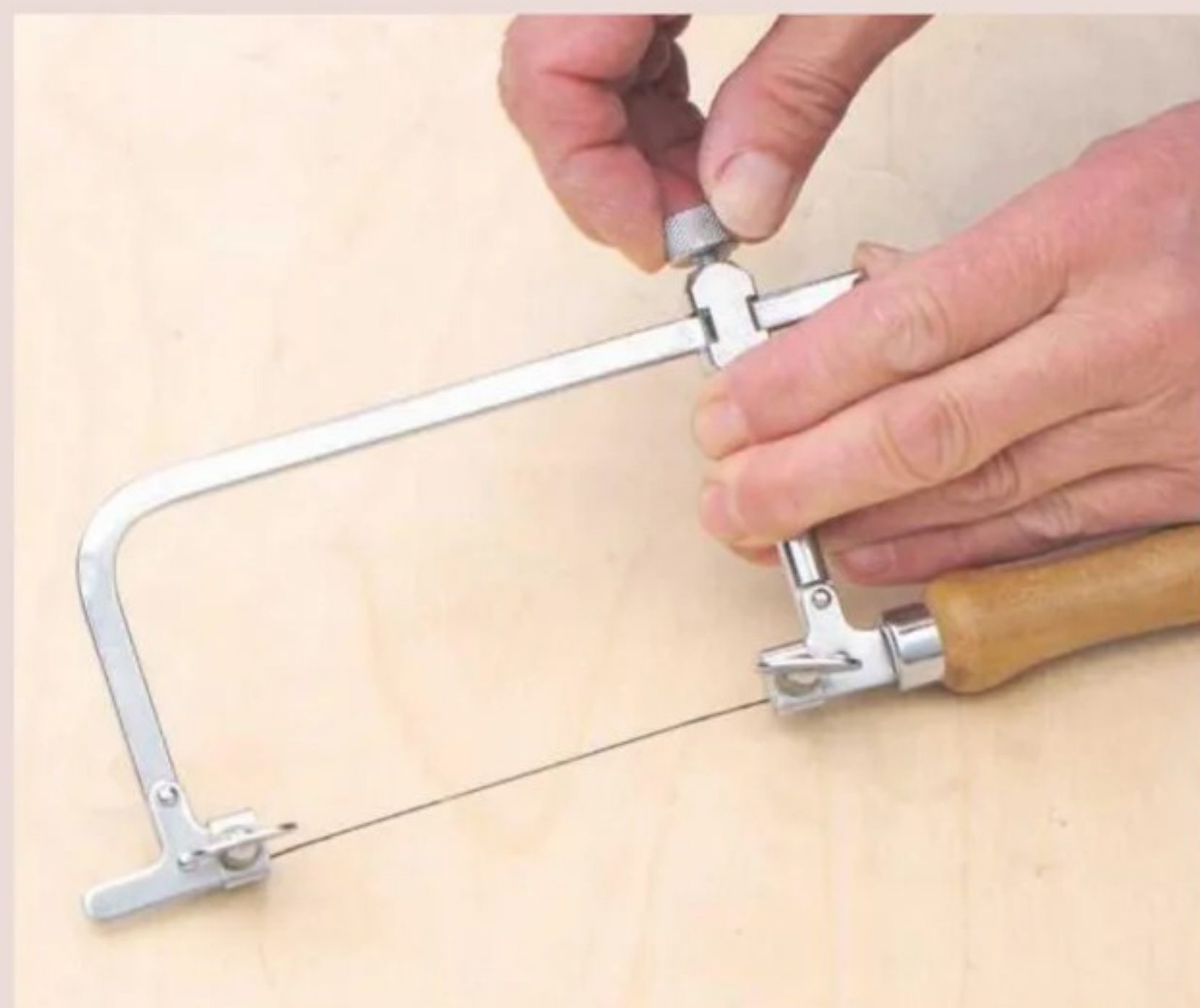
2 Slackening off the knurled thumb wheel, located on the frame, releases tension and facilitates easy blade replacement
