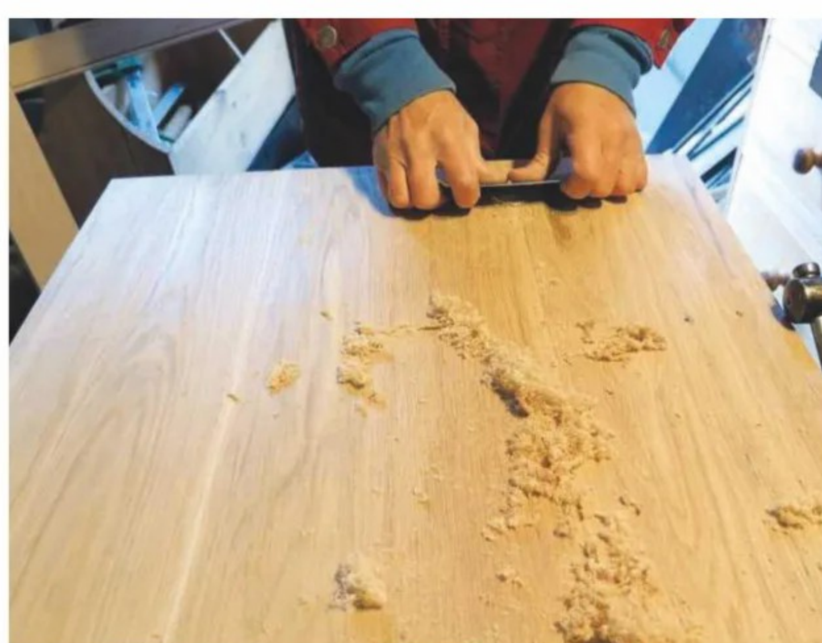
9 A cabinet scraper is used to finish the solid oak board
