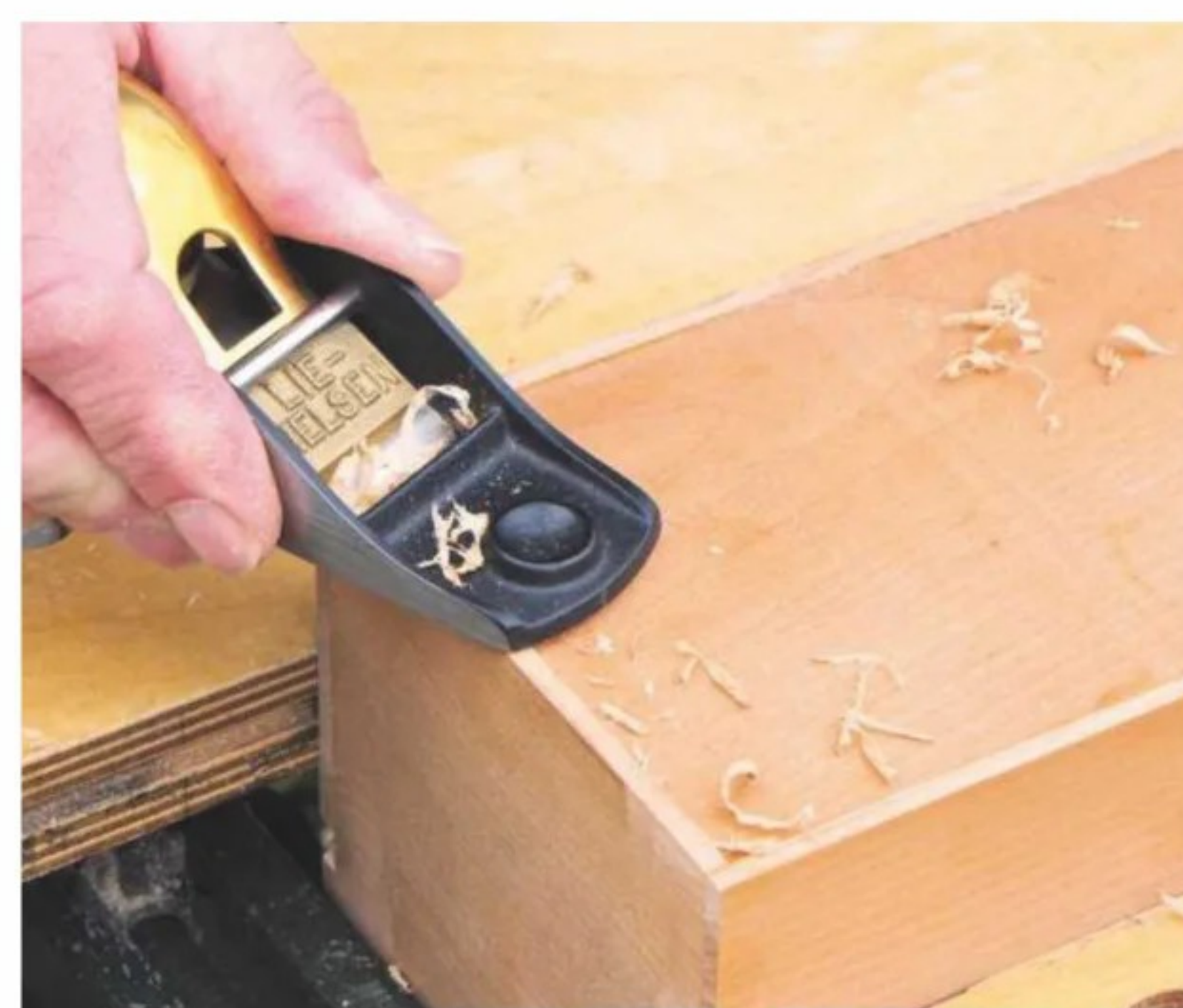
15 With the box held upside down, plane panel edges flush with the base
