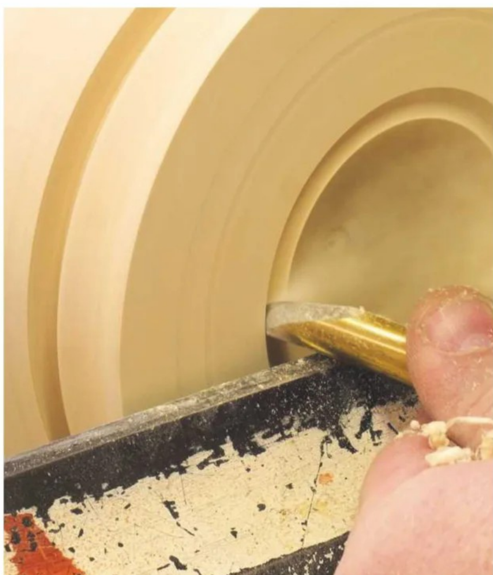
14 Using a 12mm bowl gouge, begin to hollow out the bowl interior, starting with the tool held at right angles to the surface
