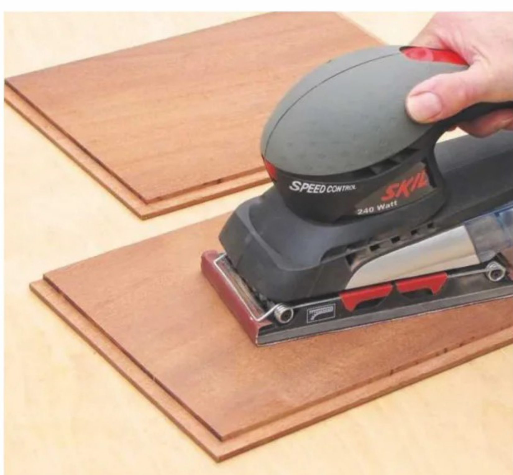
8 Sand inner surfaces with 180 grit abrasive or finer before assembling the box
