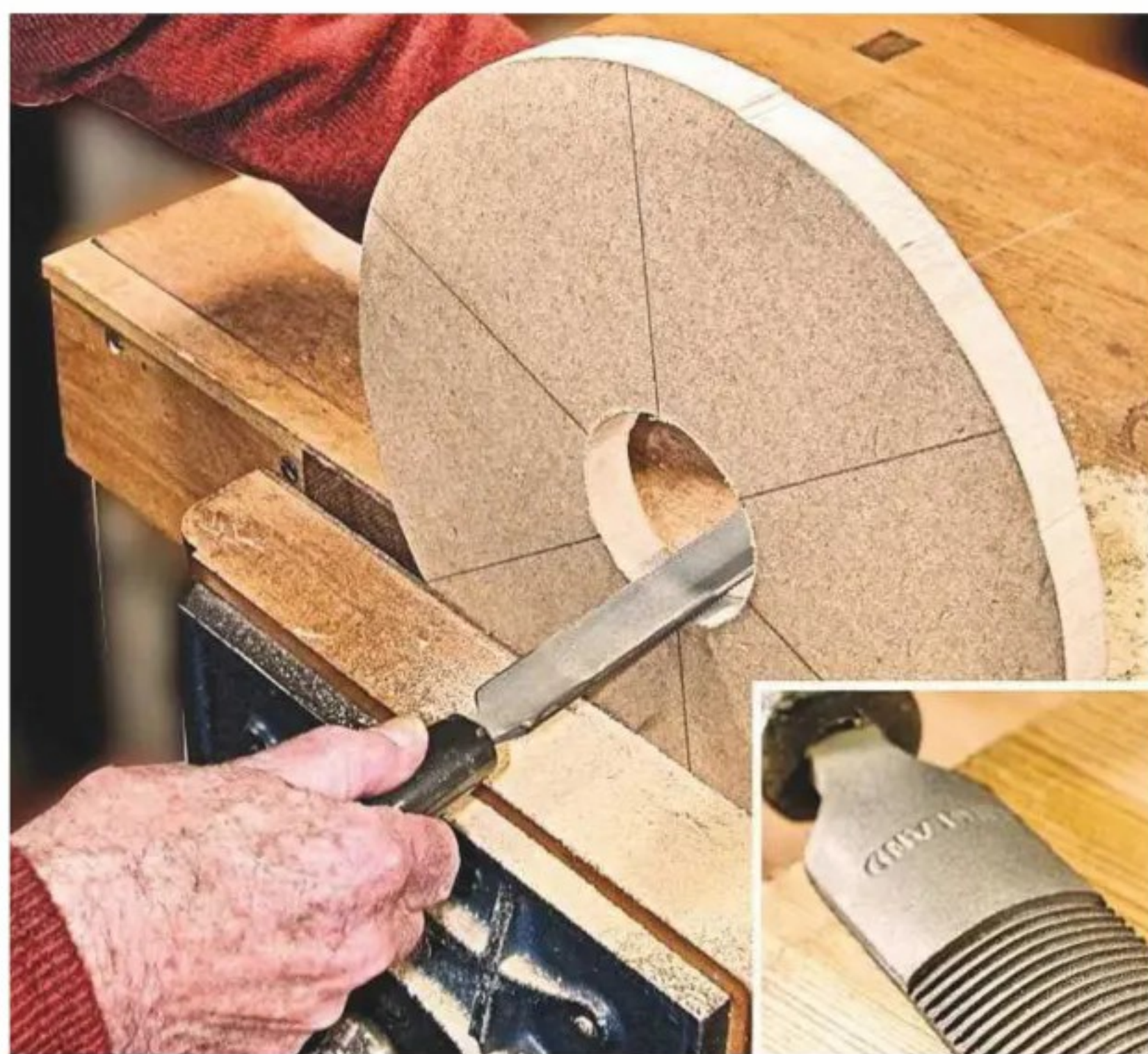
6 The dreadnought file – float – was soon filed down to the cut line made by the compass
