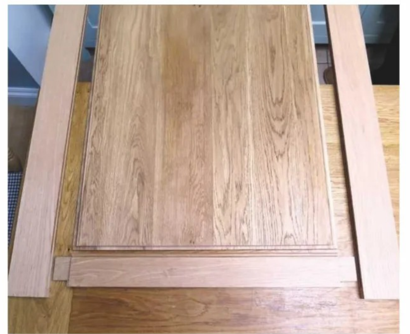
14 Main board components prior to gluing up
