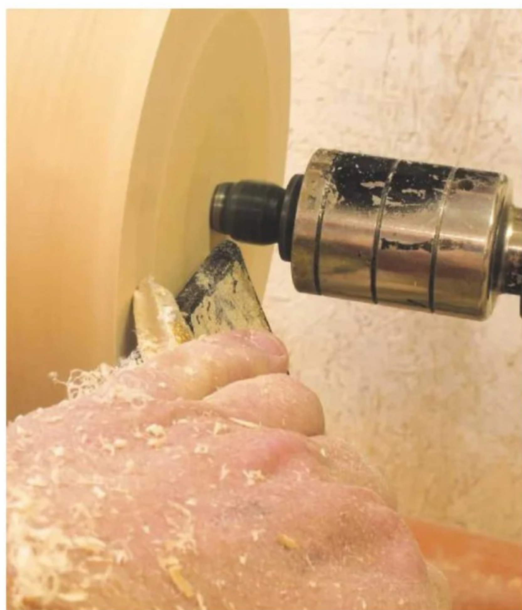
9 Mount on the chuck and true up using the same method as for flattening the base; this allows you to set the bowl's height
