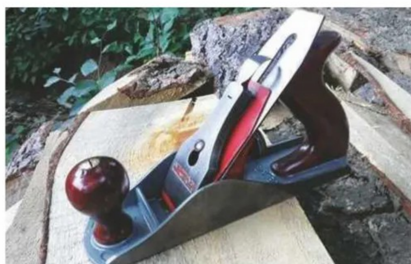
The japanned finish on these Victor planes has a 'black-hole' like depth
