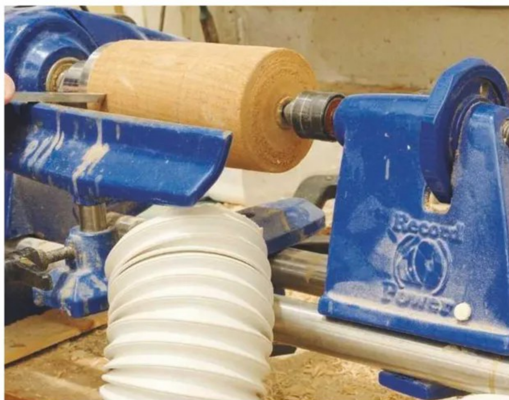
5 Lathes rapidly produce shavings and chips, which can be collected in a duct below
