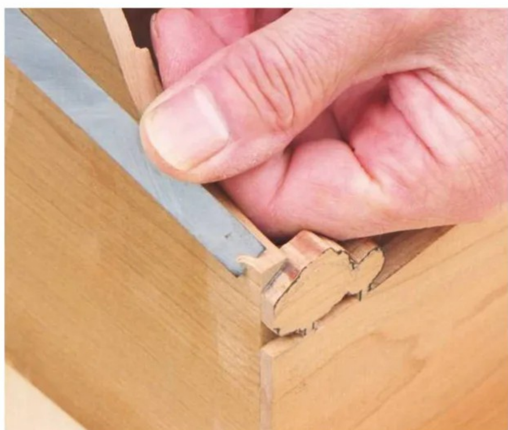
16 If the upper edges meet at slightly different heights, use a sharp chisel to contour these
