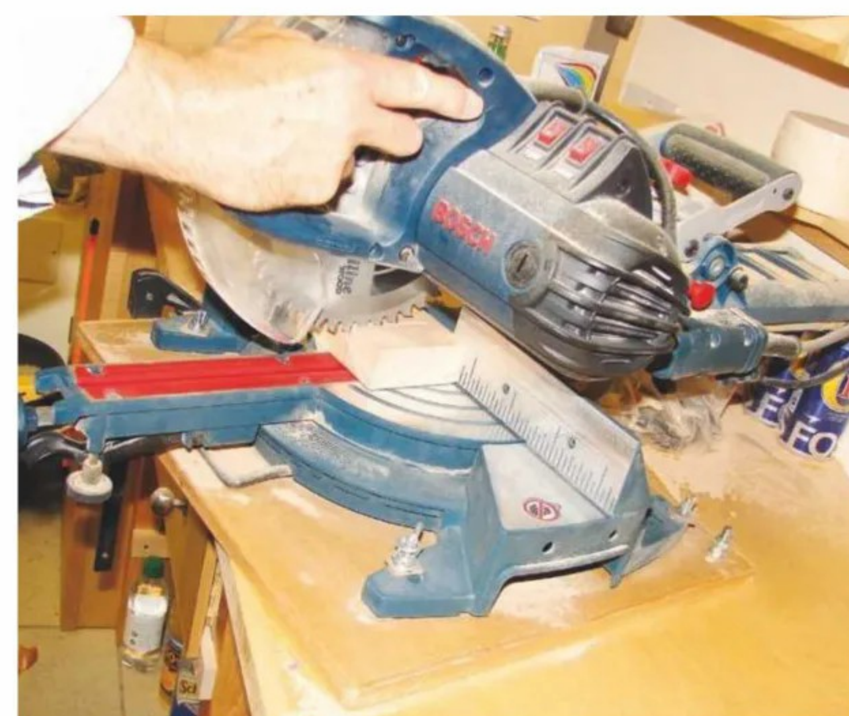
3 Tenons were dealt with using the sliding mitre saw, along with a depth stop
