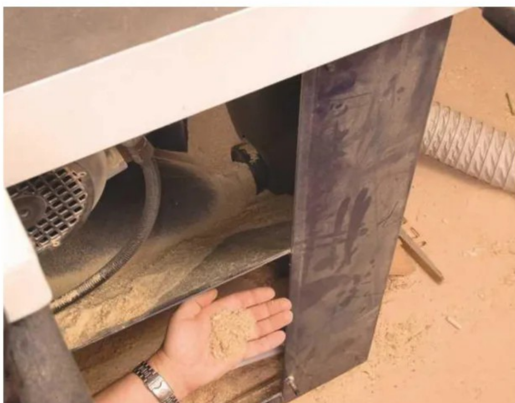
3 Here, the majority of dust is dragged down below the table, where much of it settles
