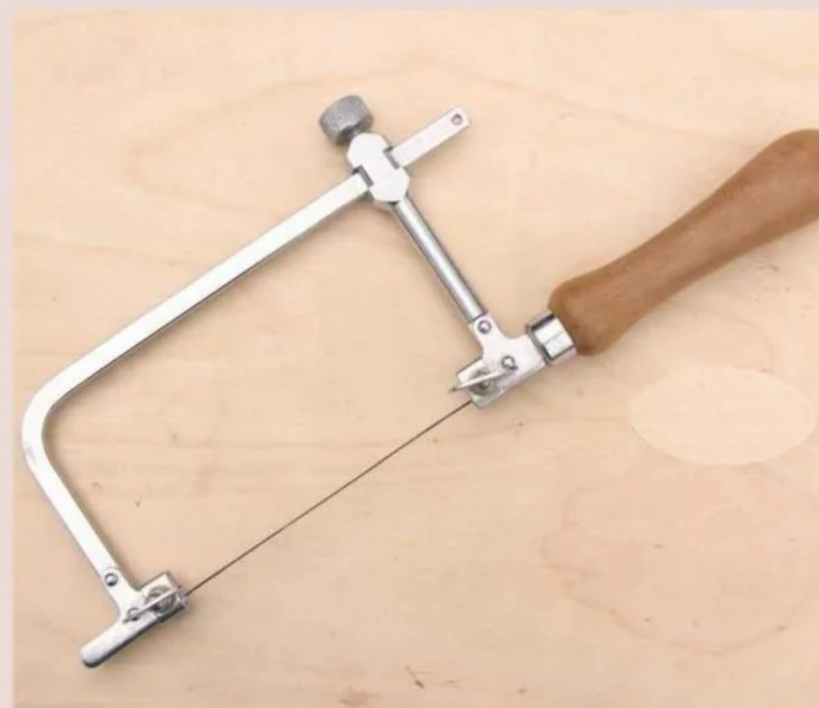
1 A piercing saw can be used for intricate shapes, though its blade can't be rotated. This is secured in place with two thumbscrews
