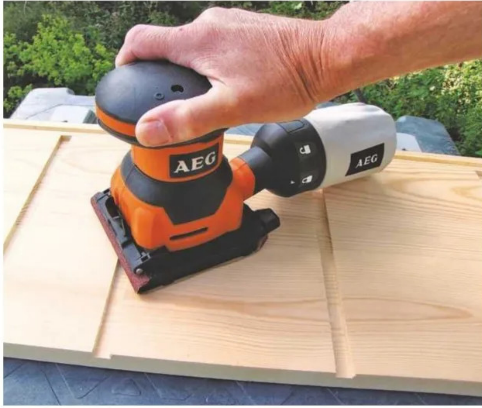
13 It's easier to sand all inner surfaces before gluing the carcass sections together
