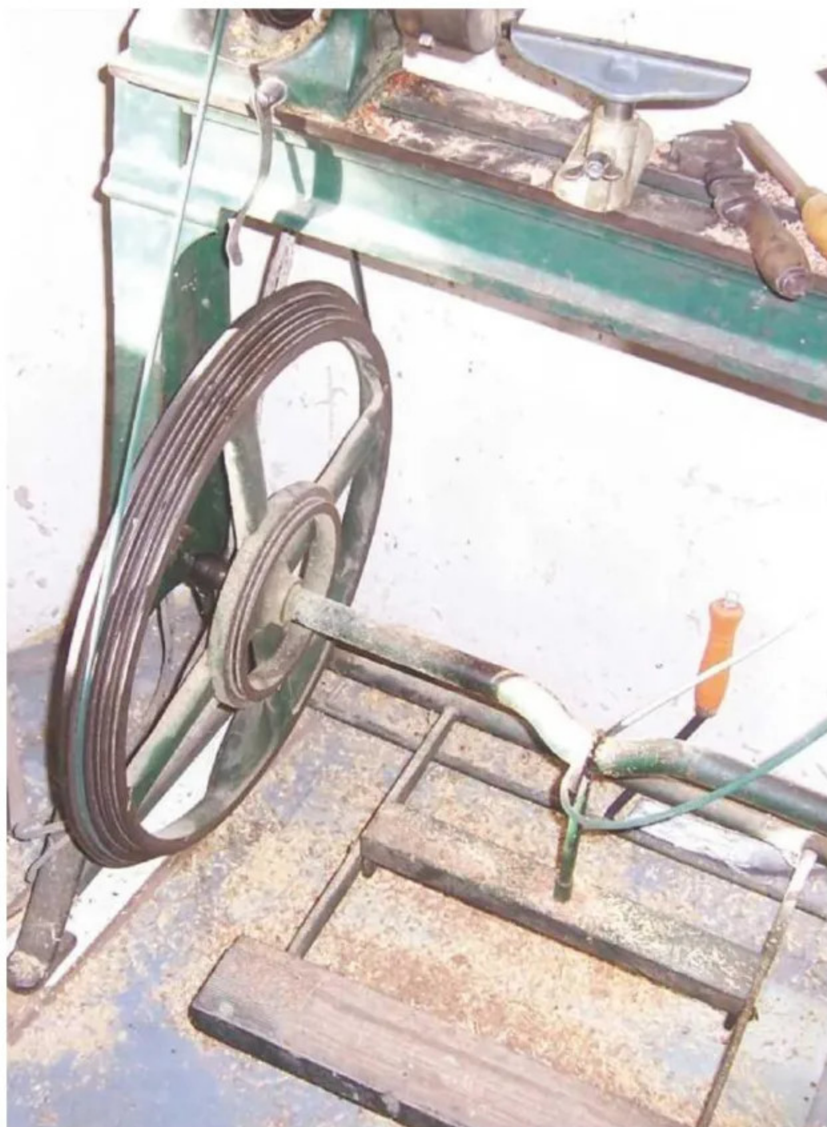
12 The lathe's cast-iron flywheel
