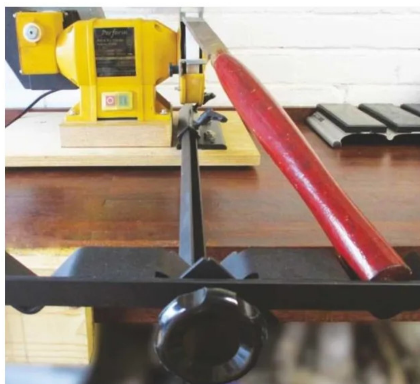
Skew chisel set up – power off, correct screw!
