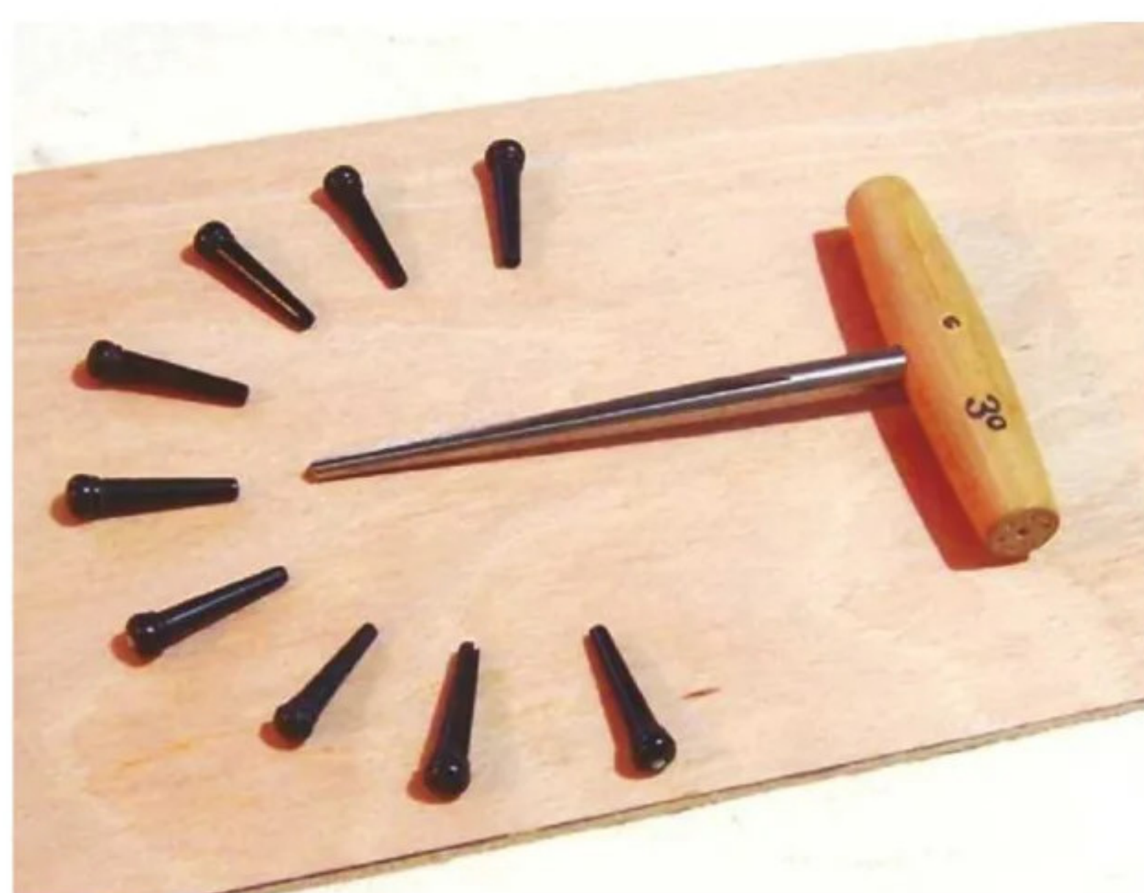
9 Bridge pins with a 3° reamer
