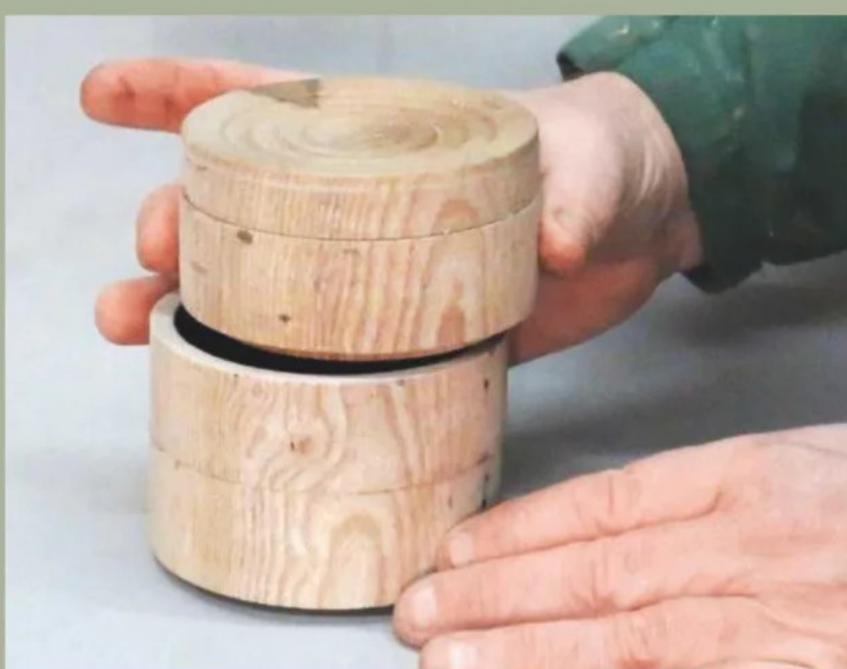
24 To ensure that each of the tiers opens freely, check that the rod moves in the stepped hole
