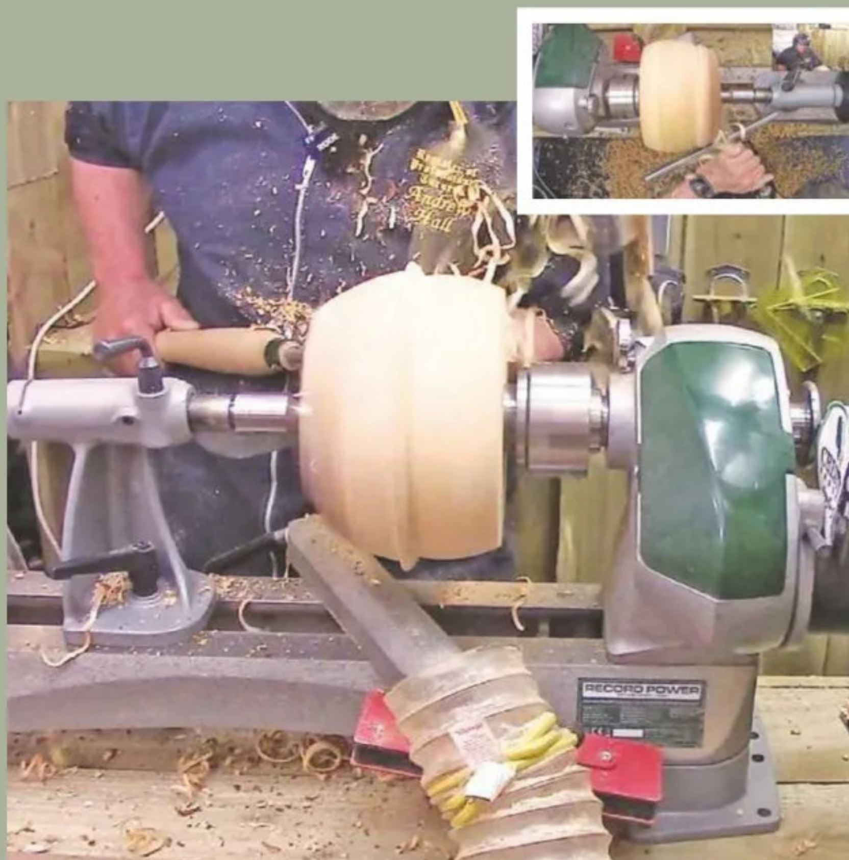
9 Creating a nice flowing shape isn't always easy to achieve, but I find that locking the tool into the side of my body and using a body rather than arm movement, creates a nicer shape
