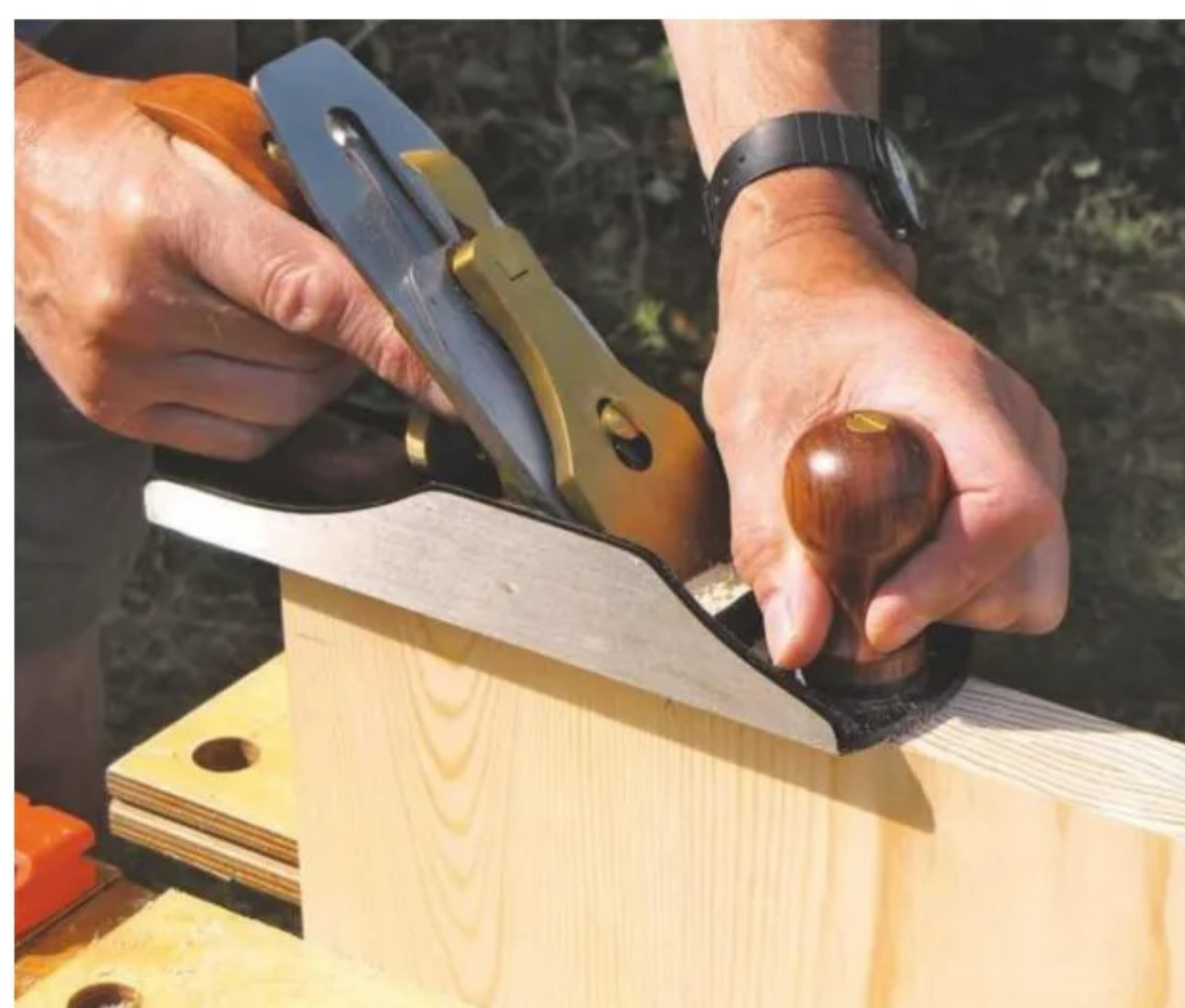
5 Cramp both pieces together and plane end-grain square, working towards the centre for best results
