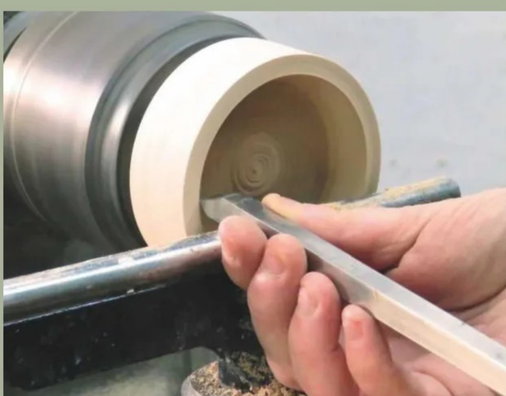
12 Use a scraper to square up the hollow's side and flatten the bottom
