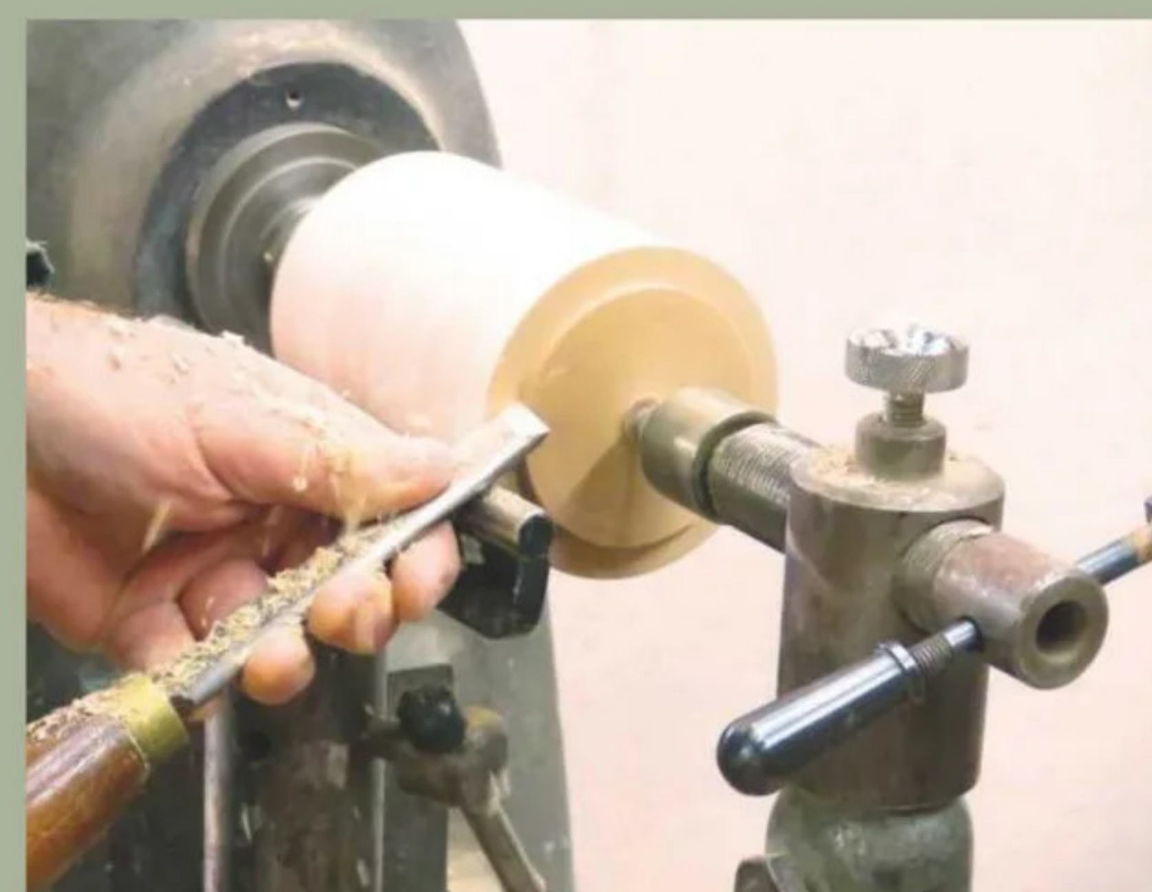
2 Square off one end and cut a chucking spigot
