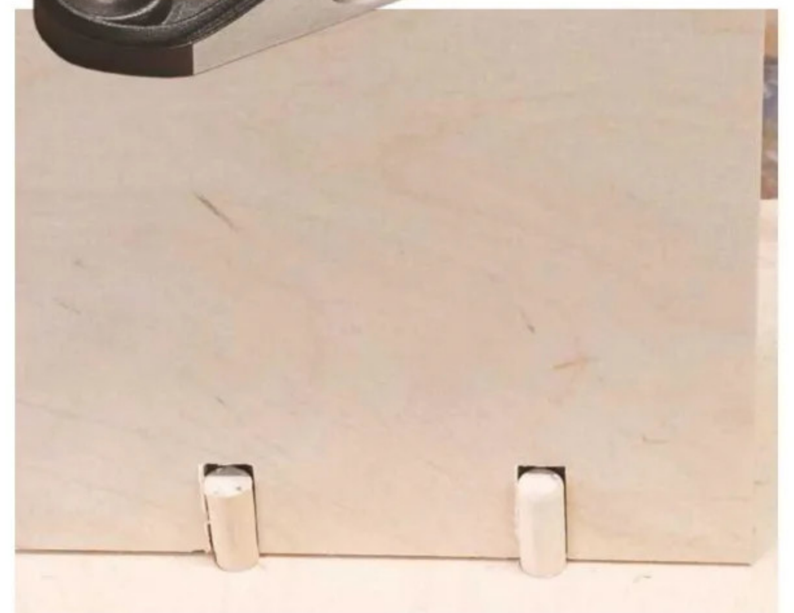
3 Shelf underside showing support dowels locked in position
