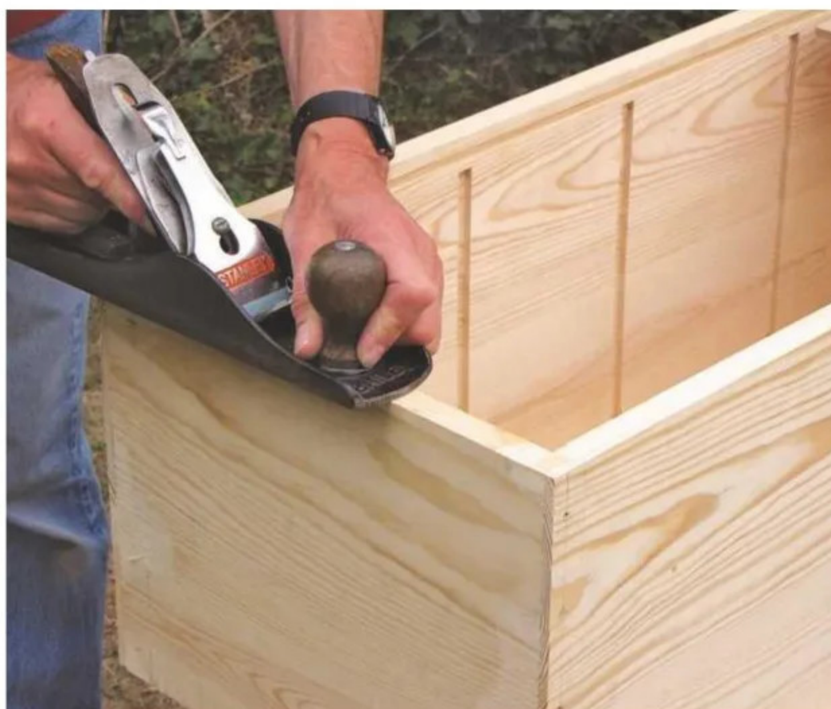
17 Using a plane, clean up excess end-grain from the lap joints, then shoot the front and rear edges
