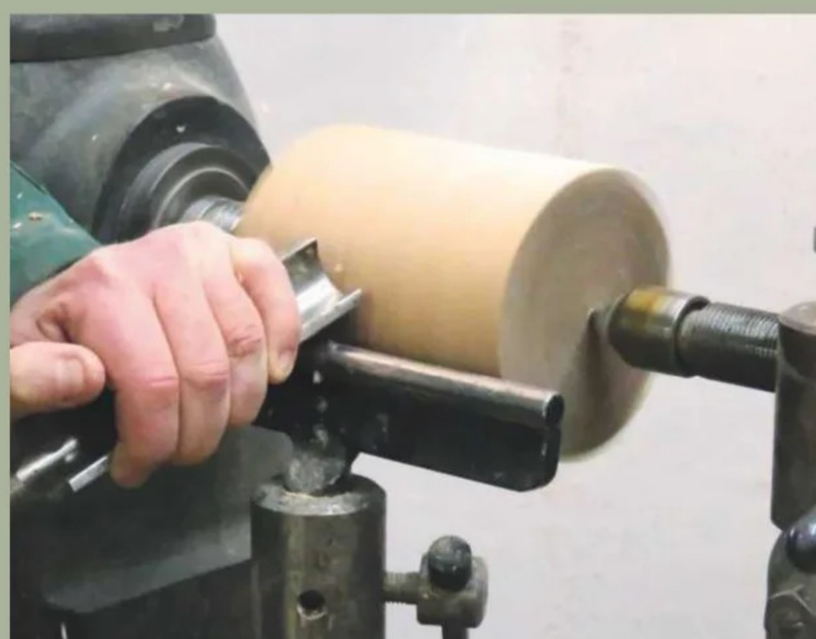
1 Mount the blank between centres and convert to a cylinder
