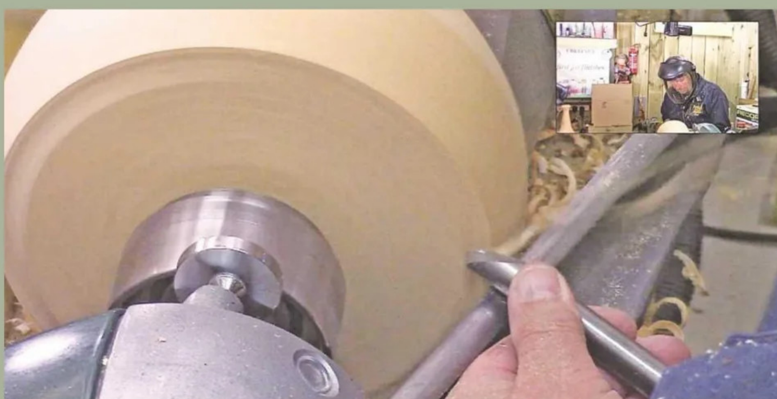
12 Next, I trued up and balanced the face surface of my bowl – so it at least matched the rim's width – using the wing's bottom third on the 12mm swept-back bowl gouge. Here I'm stood at the headstock side of the lathe, which allows the shavings to disperse and also helps to capture a clear image
