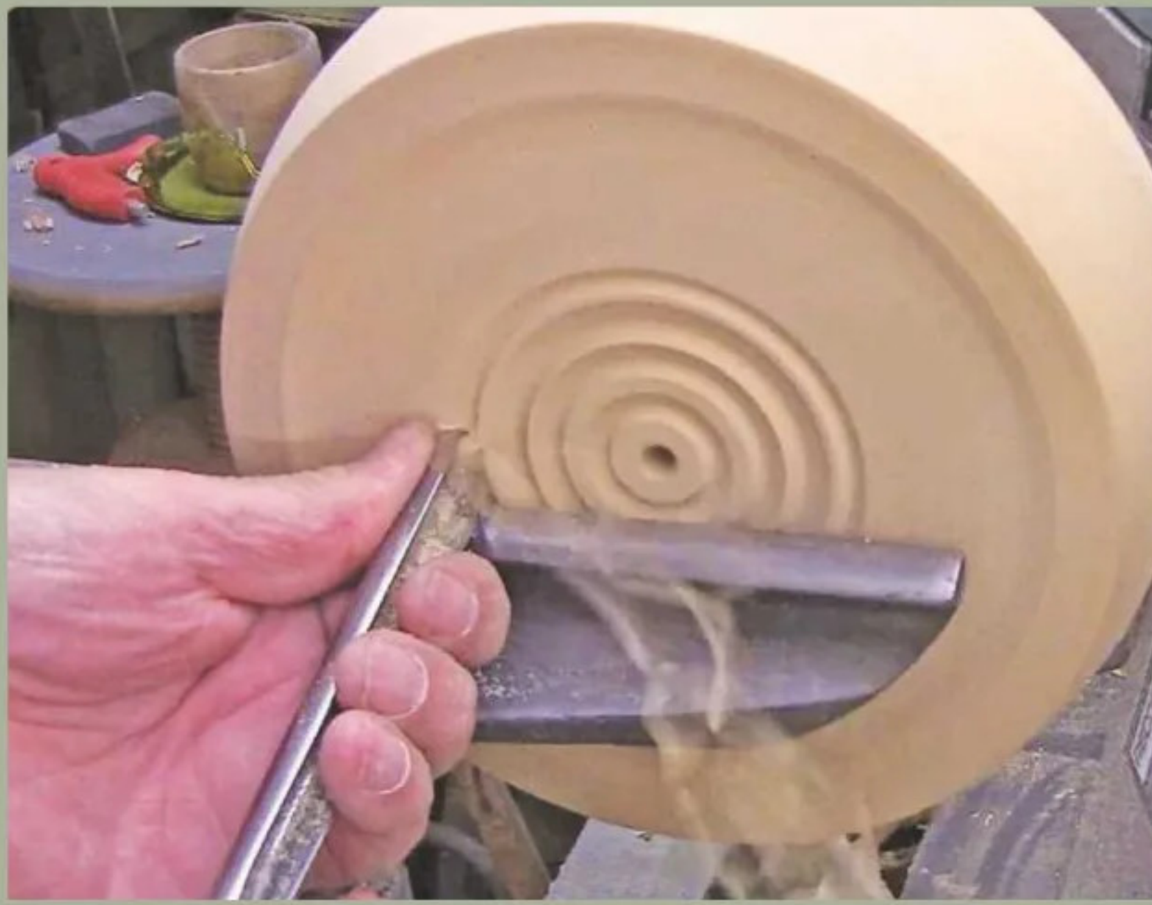
15 Using the 12mm swept-back bowl gouge as before, I created a series of 'V' cuts, allowing for the tool's bevel to make contact with the material while hollowing, and thus preventing skate back
