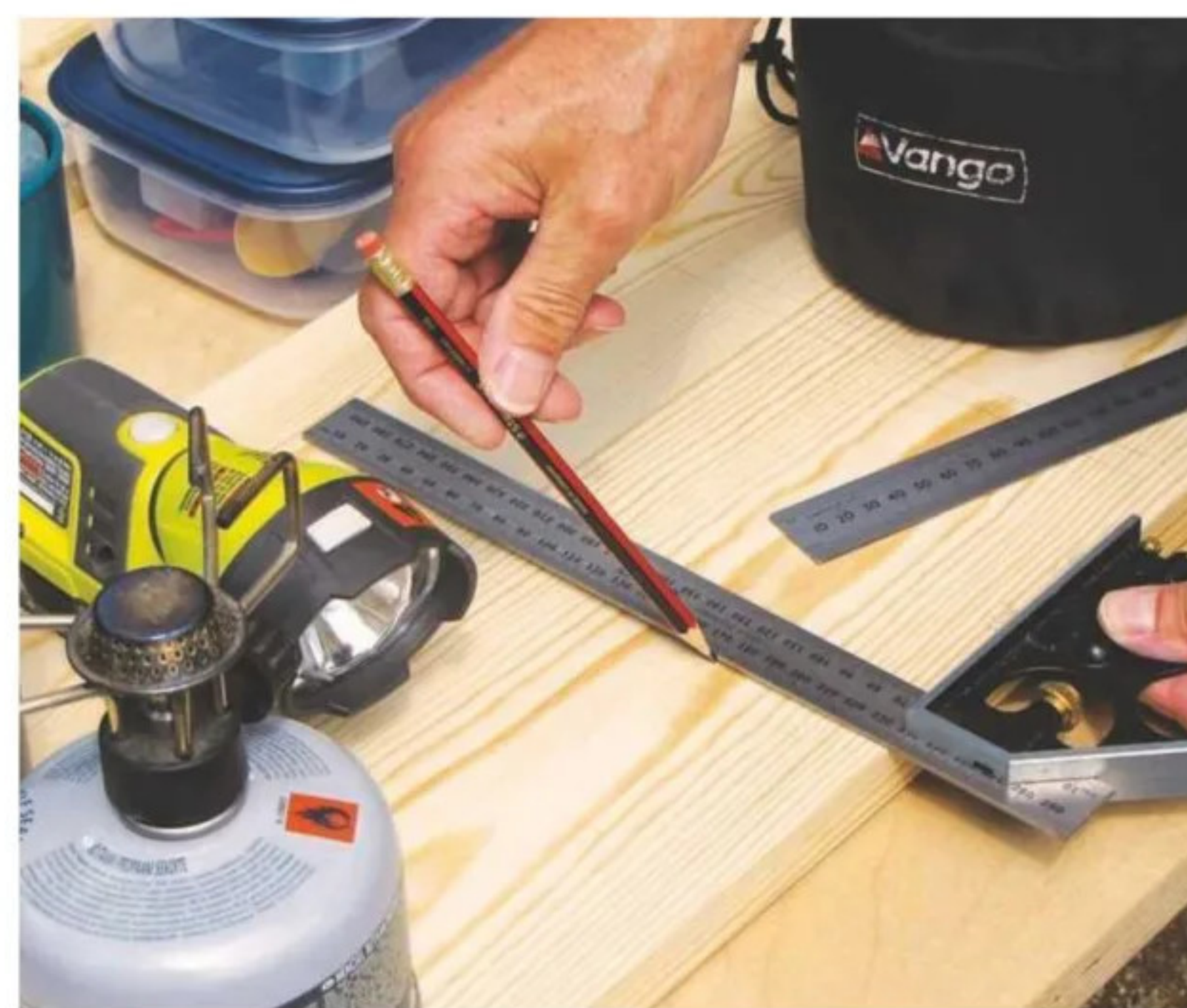
9 Place utensils where you want them and mark out positions for divider panels, using 12mm MDF
