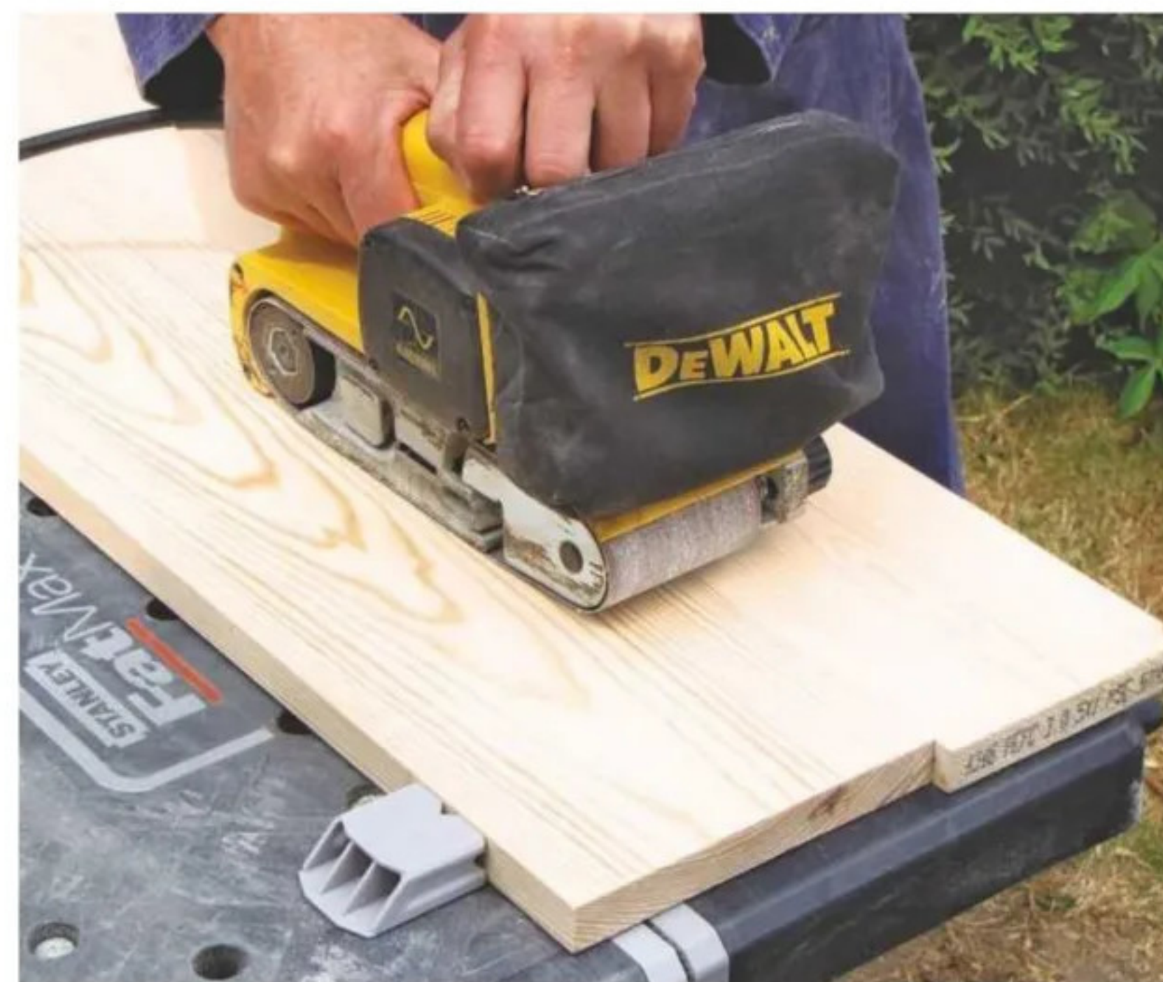
3 Once the glue is dry, sand the boards, or better still, pass them through a wide thicknesser
