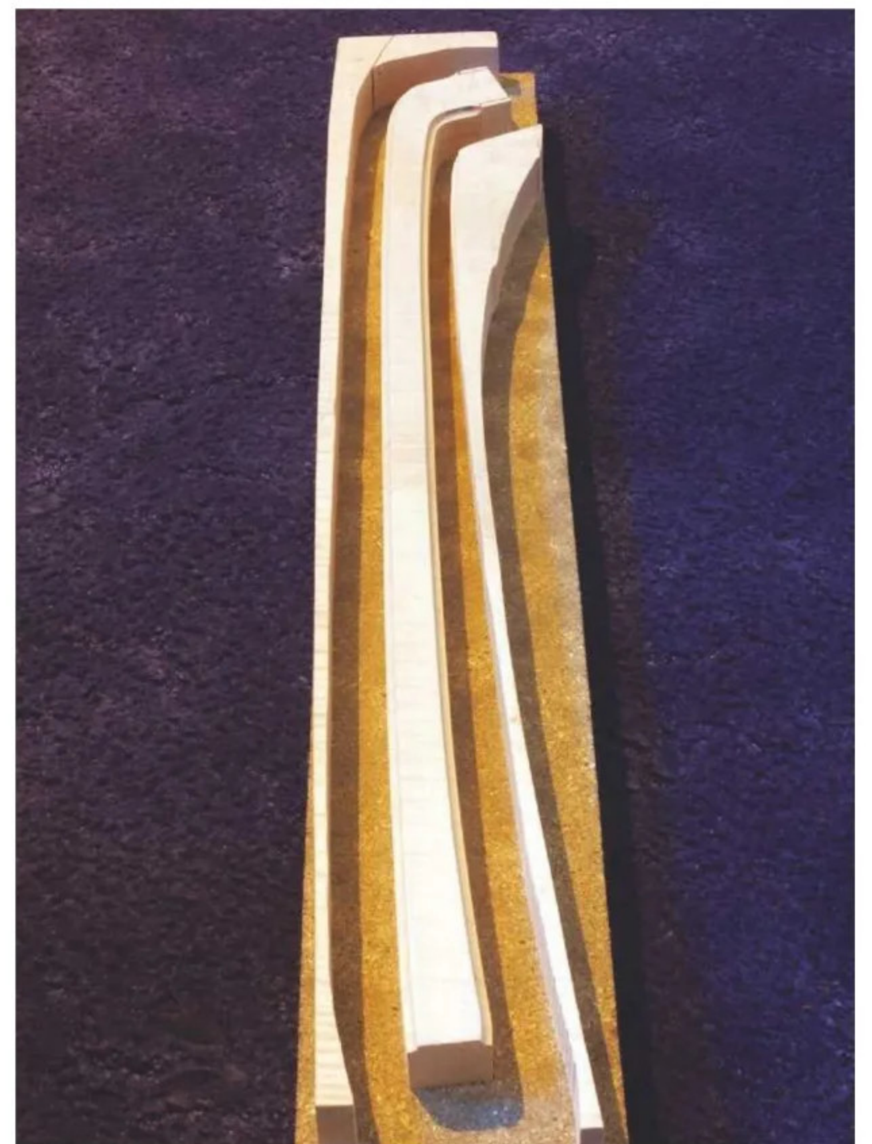
13 Side supports in place, which help with cutting accurate flutes in the pillar
