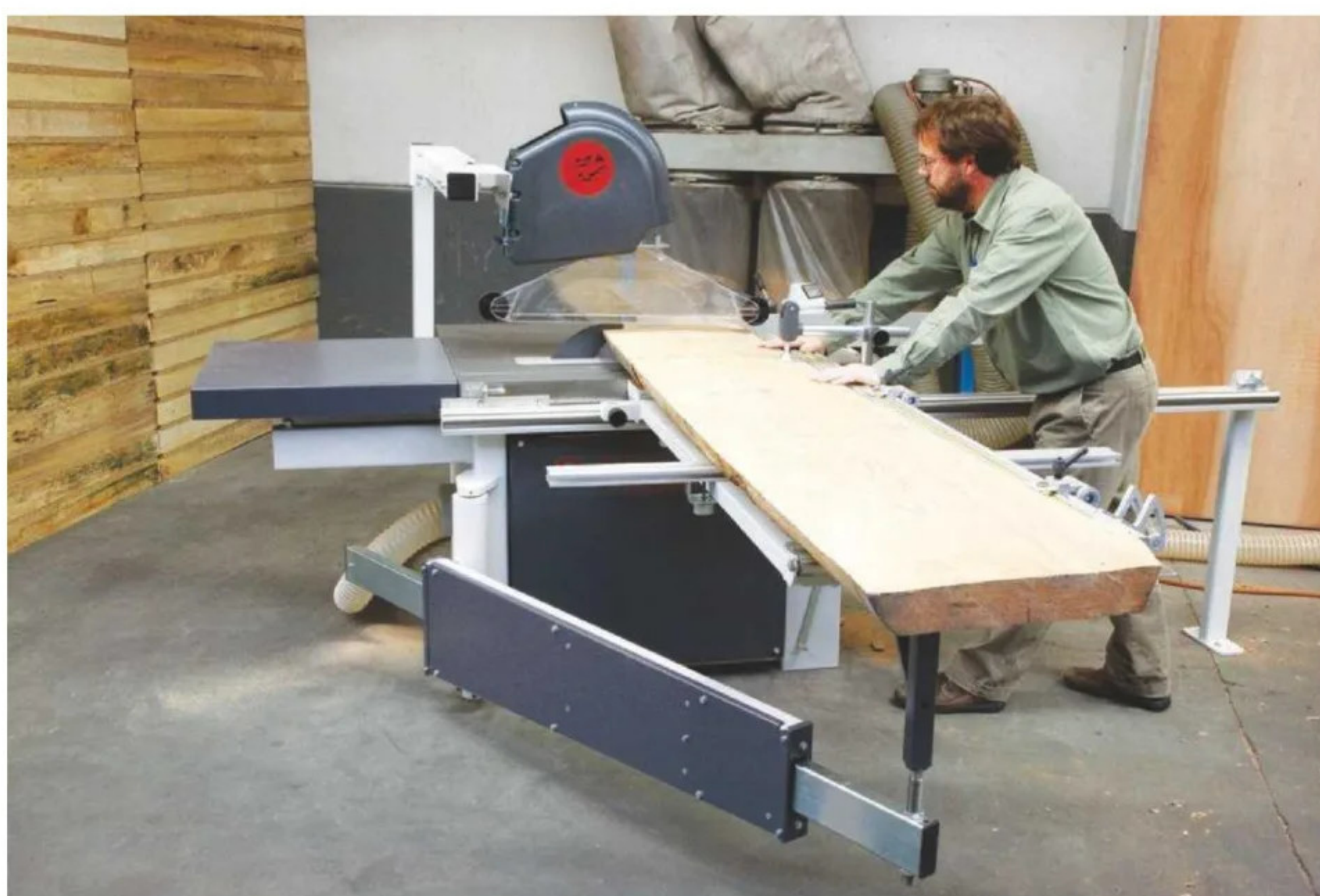
11 This seriously heavy-duty dimension saw is the size and weight of a small car, while its swinging arm offers support when cross-cutting large pieces of timber
