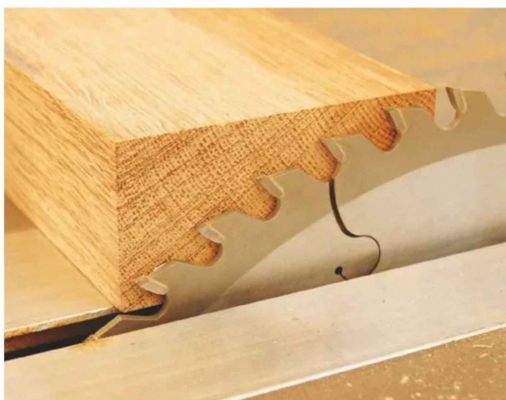
3 Blade height is adjusted slightly higher than the wood's thickness; this ensures the maximum number of teeth are in contact
