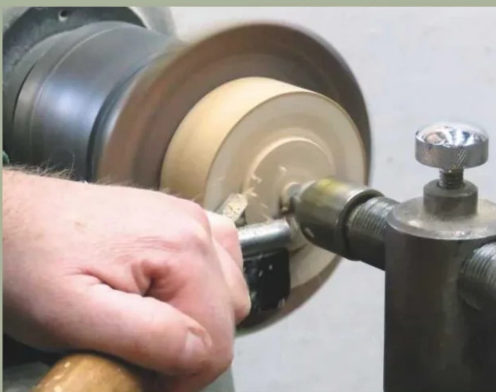
19 Reverse chuck the base onto a dolly so you can remove the chucking spigot
