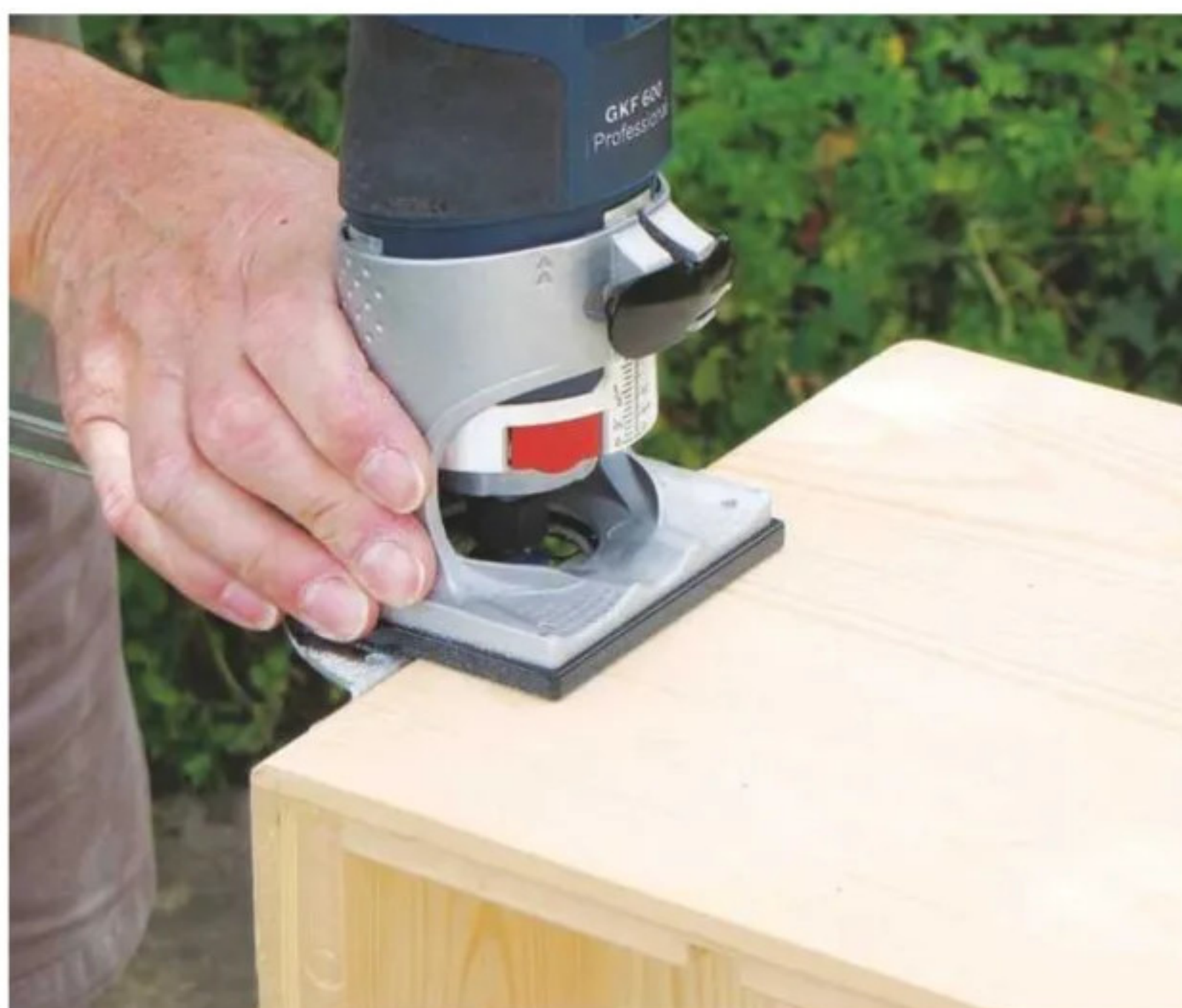
20 Using a round-over bit, rout all outer edges in order to soften the cabinet
