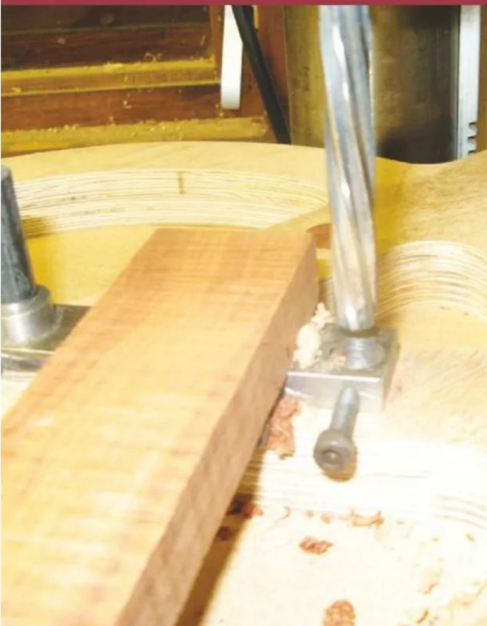
Hole finished off with a 10mm reamer
