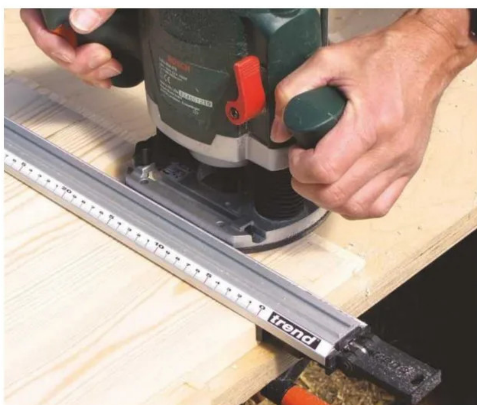
7 To create the join, using a straight cutter, rout a rebate at each end of both top and bottom panels
