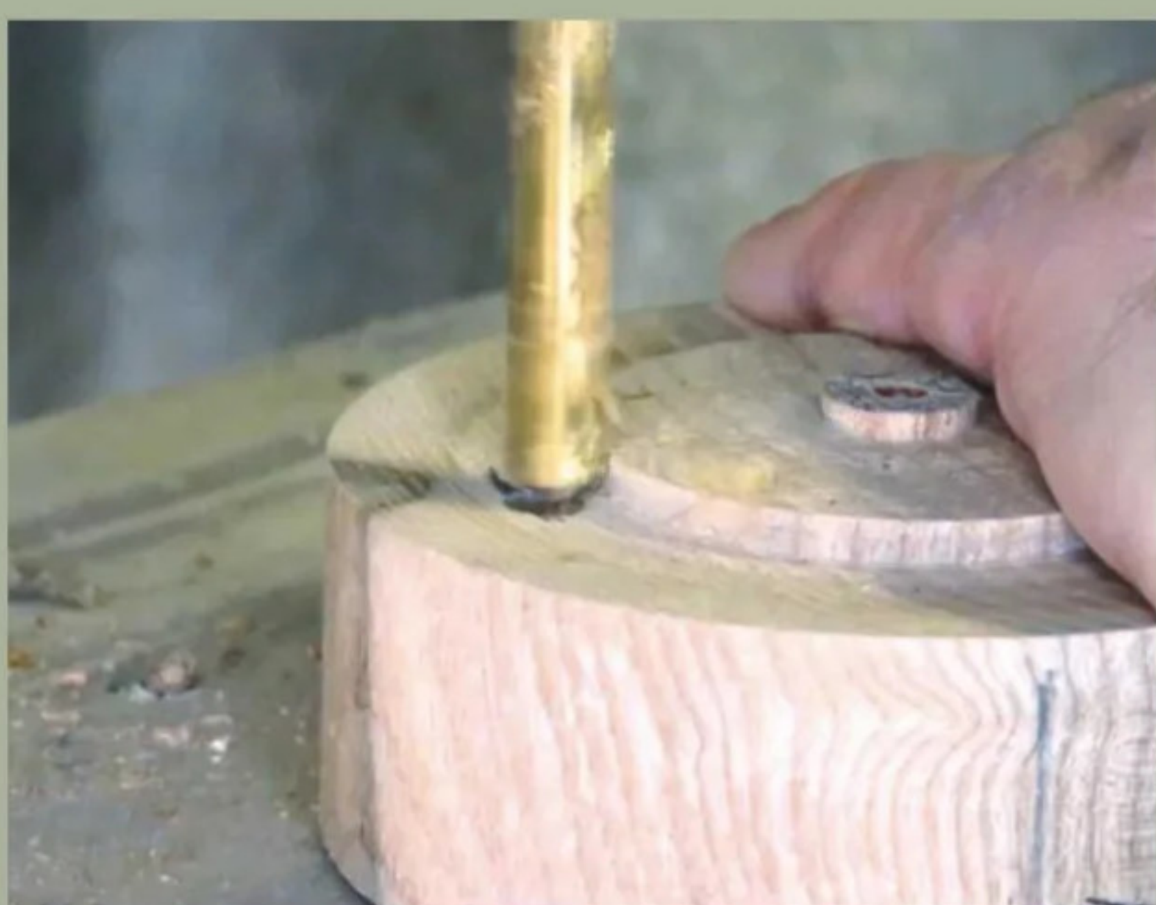
21 Drill an 8mm counterbore on the base's underside, which is about 6mm deep
