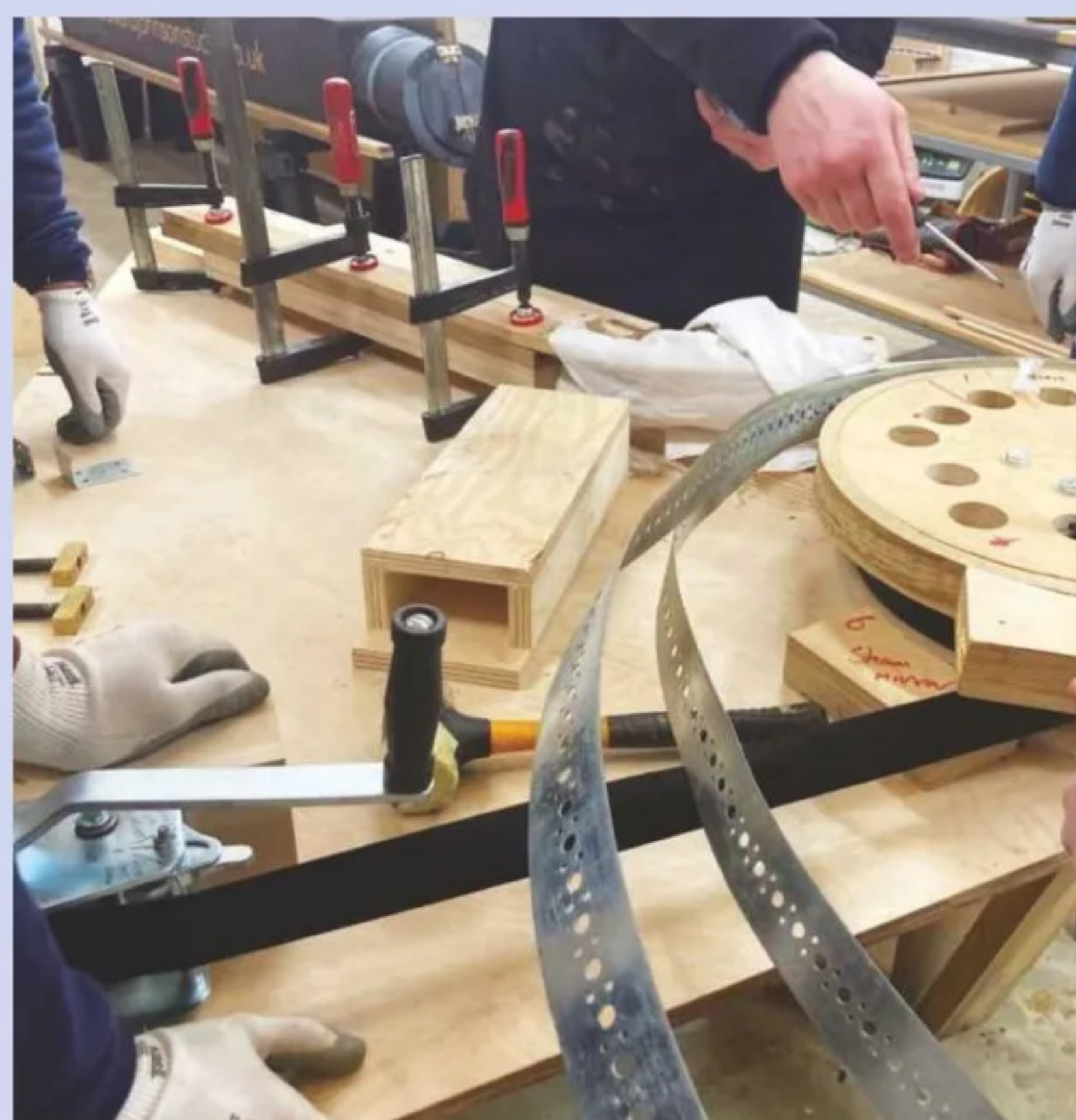
Steam-bending in progress on the five-day 'Make your own Sussex Mirror' course
