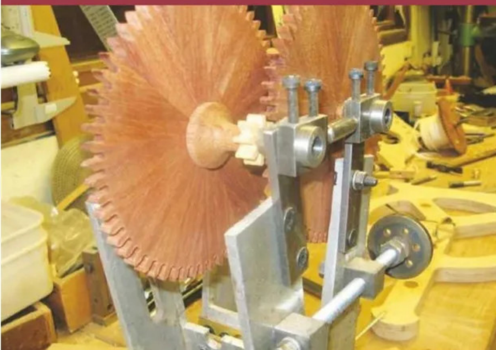
Wheels having been adjusted to achieve a good mesh. The pinch rod can now be used to transfer this precise distance to the frames
