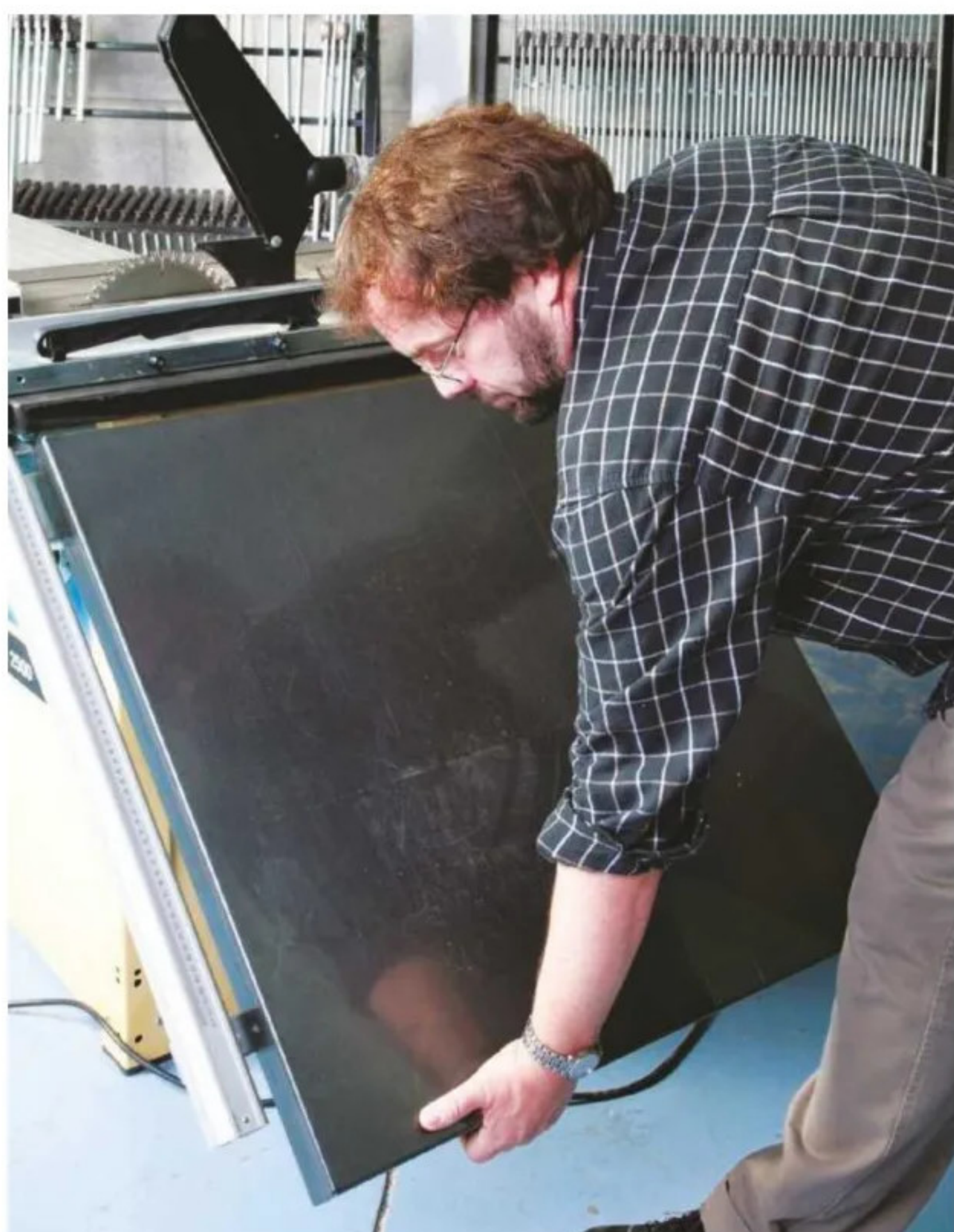
8 Small saws may come with table extensions either fitted or as optional extras; these allow larger boards to be handled
