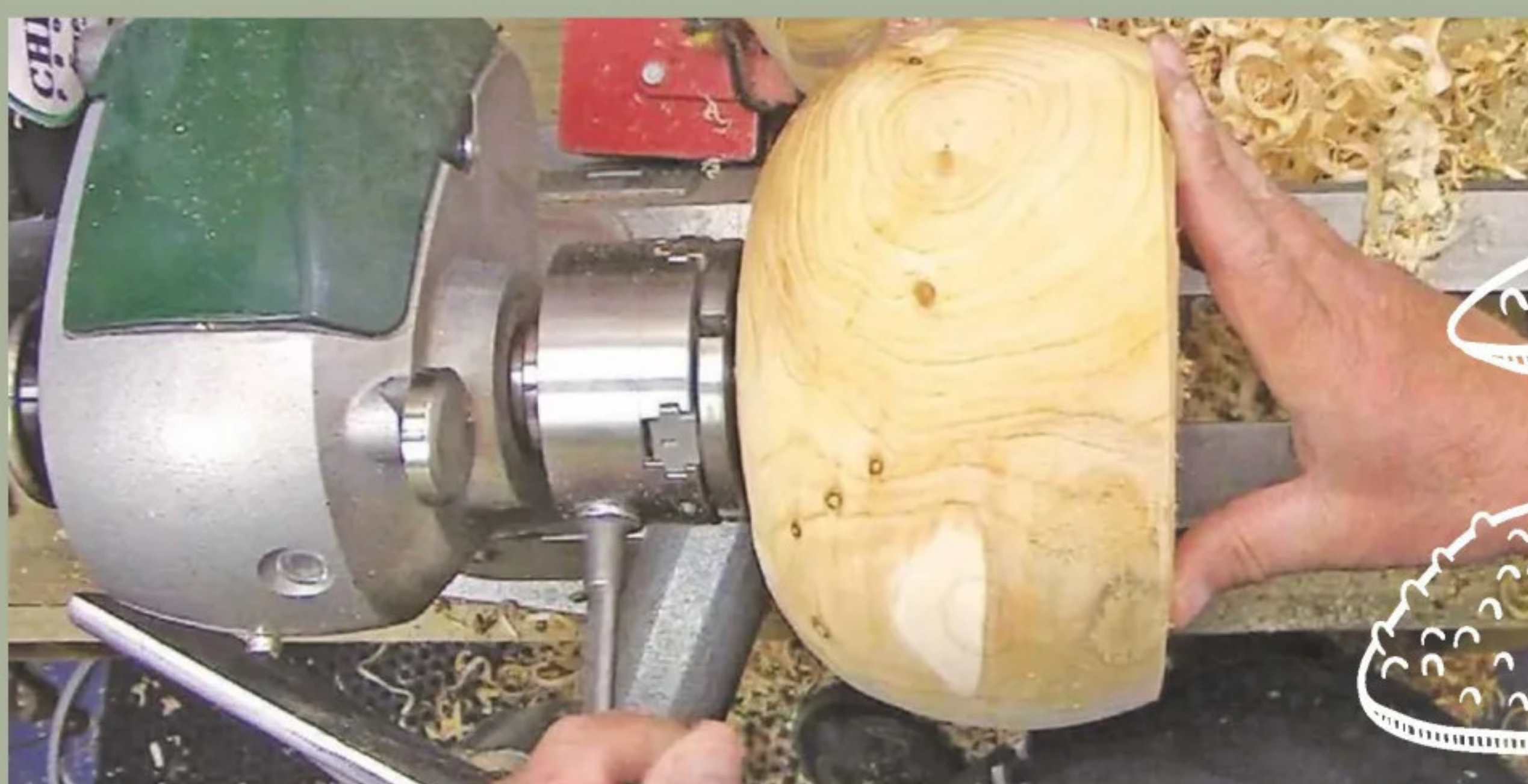
14 Having achieved the best possible finish on the material, I turned the bowl around and held it in the chuck jaws, cutting a recess to match the jaws' optimum circle size
