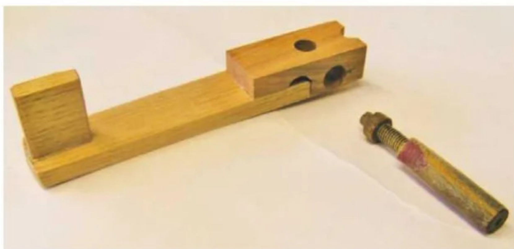
Clock crutch and 12mm diameter lignum vitae cotter pin with offset 8mm diameter thread on the end
