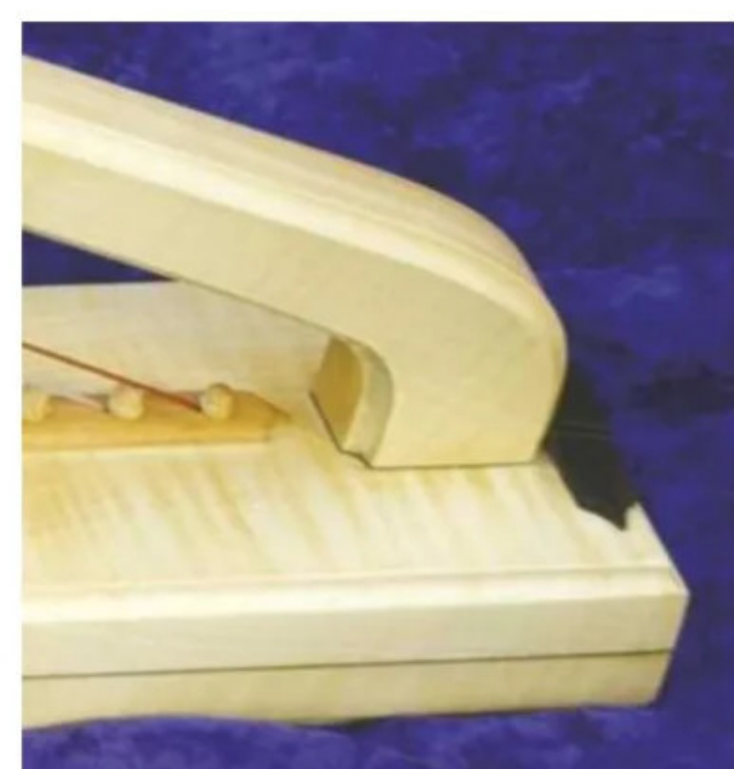
16 An ebony block keeps the lower mortise & tenon joint fixed
