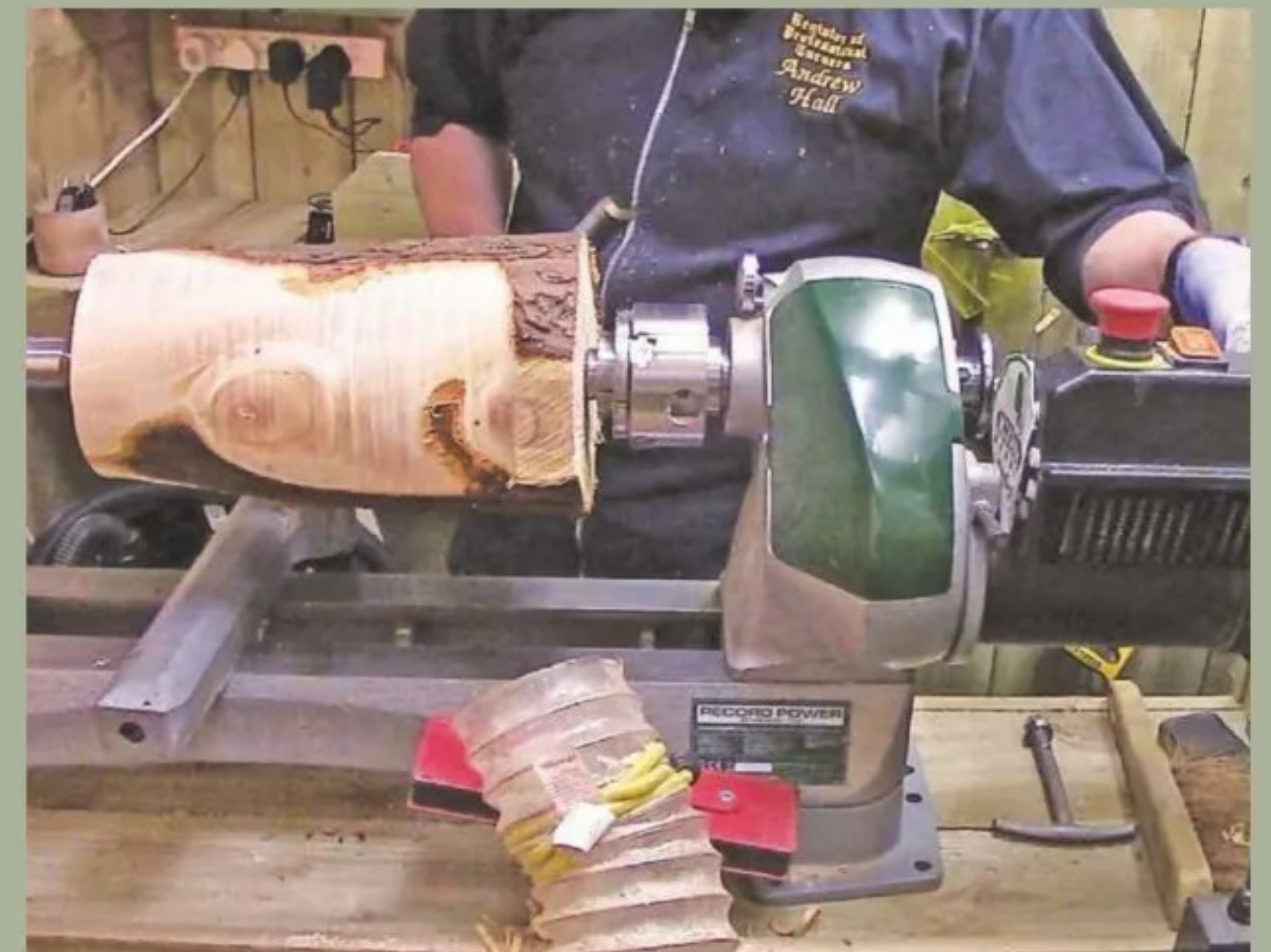
19 Here you'll notice I'm wearing a pair of blue lightweight disposable gloves. Gloves and woodturning have always sparked a debate in terms of safety and safe usage. I don't wear gloves unless the material is sticky or resinous, as with the leylandii at the beginning. If you do need to wear gloves, I suggest trying the ones shown here. Some of my friends have skin complaints, which affects their hands, so therefore always require protection. With the disposable variety, in the case of potential catches, they'd just be torn from your hand and not get wrapped in with the turned piece, which would result in the hand and fingers being dragged towards the chuck. Some pine species and monkey puzzle are notorious for their sticky sap content, and even fresh yew can be on the resinous side. Once balanced and examined for defects, I was then able to increase lathe speed
