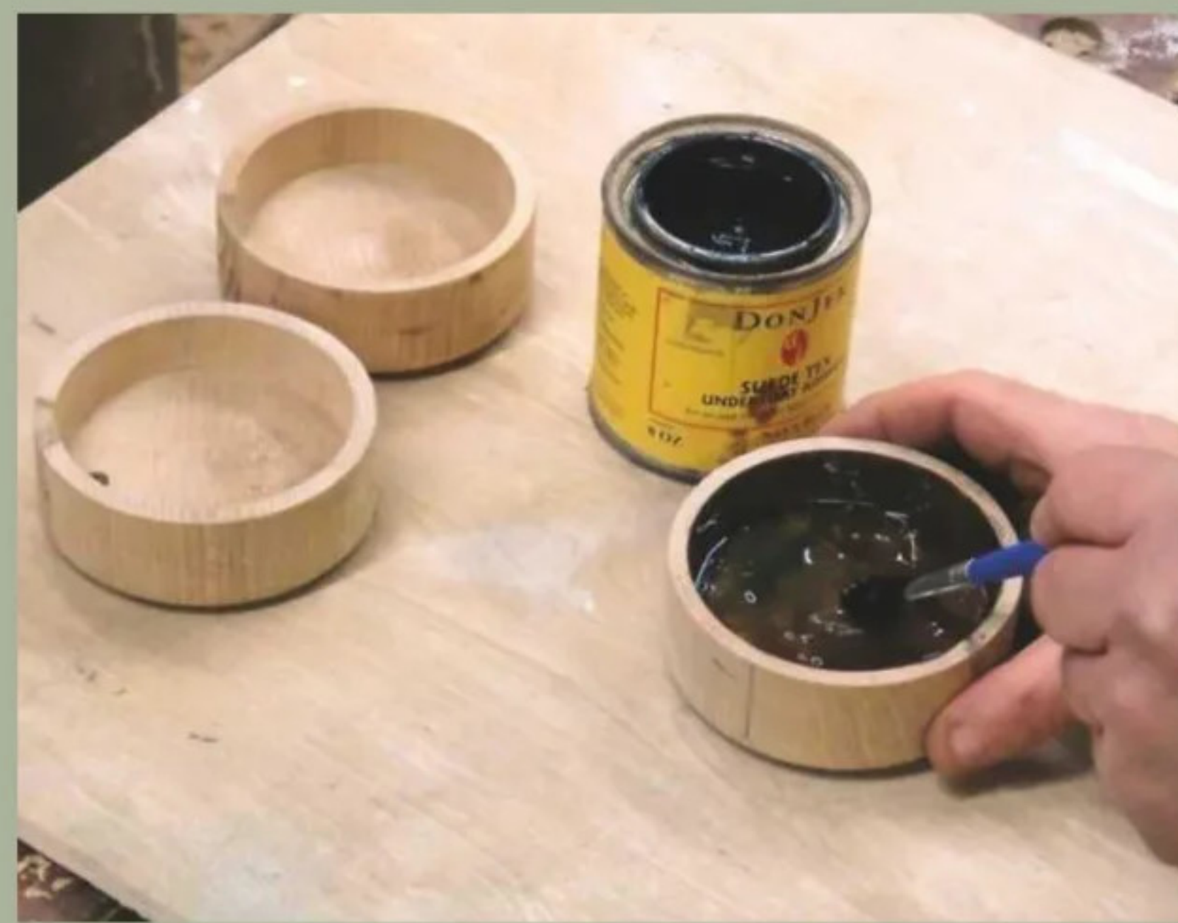
17 Paint on a generous amount of adhesive...
