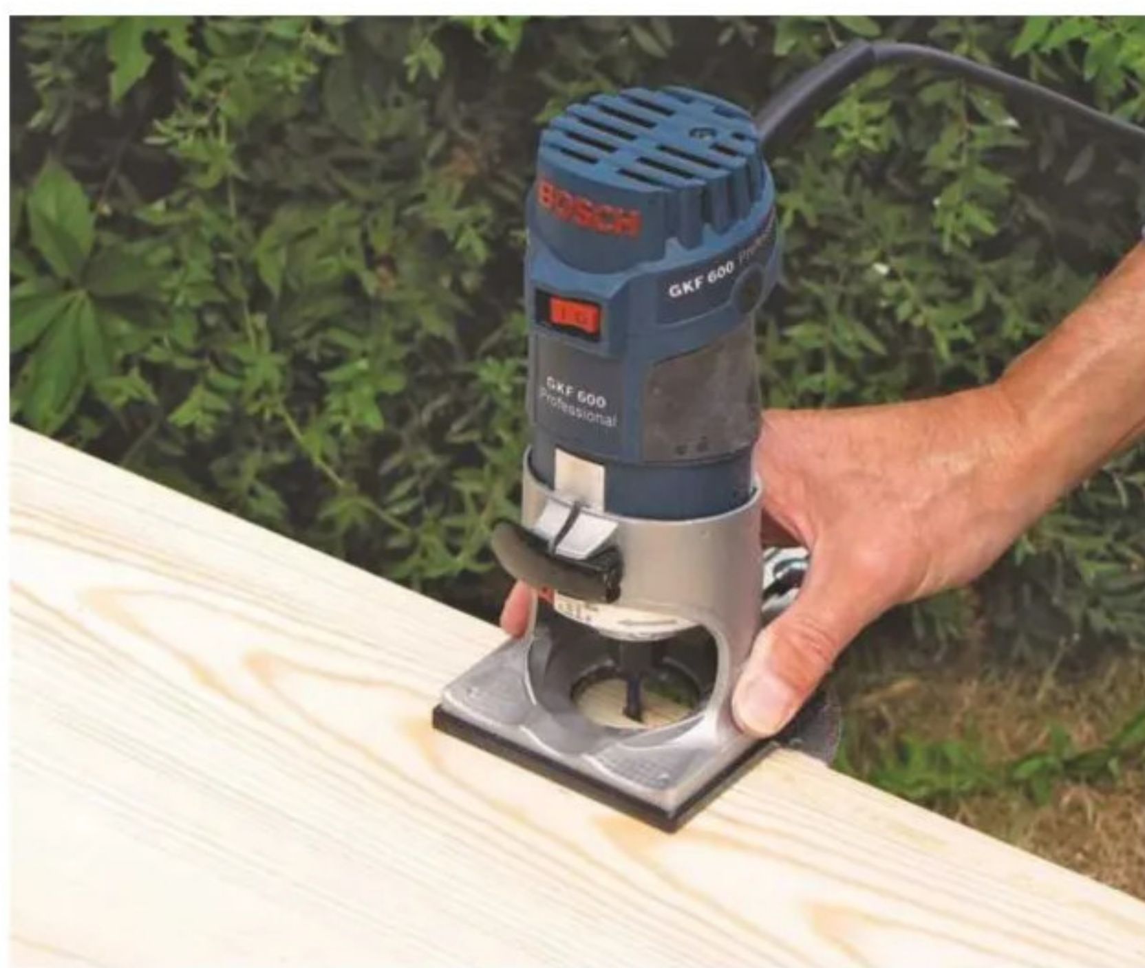
10 This box has a sliding front panel, so rout a 7mm groove along each inside edge
