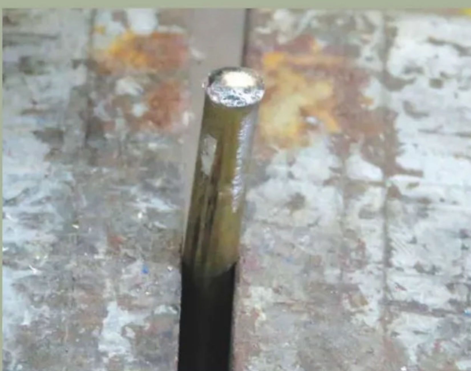
22 Flare over one end of the rod so that it's not able to go through the 6mm hole
