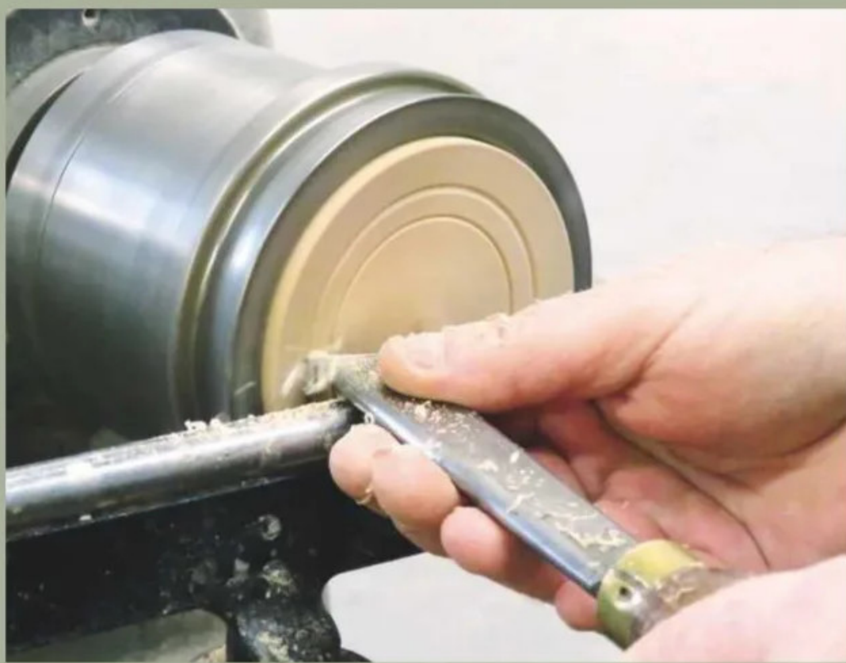
15 Using a skew chisel, cut a number of decorative beads on top of the lid
