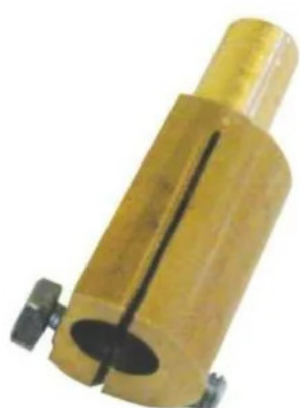
Homemade jig made to turn offset on the cotter pin
