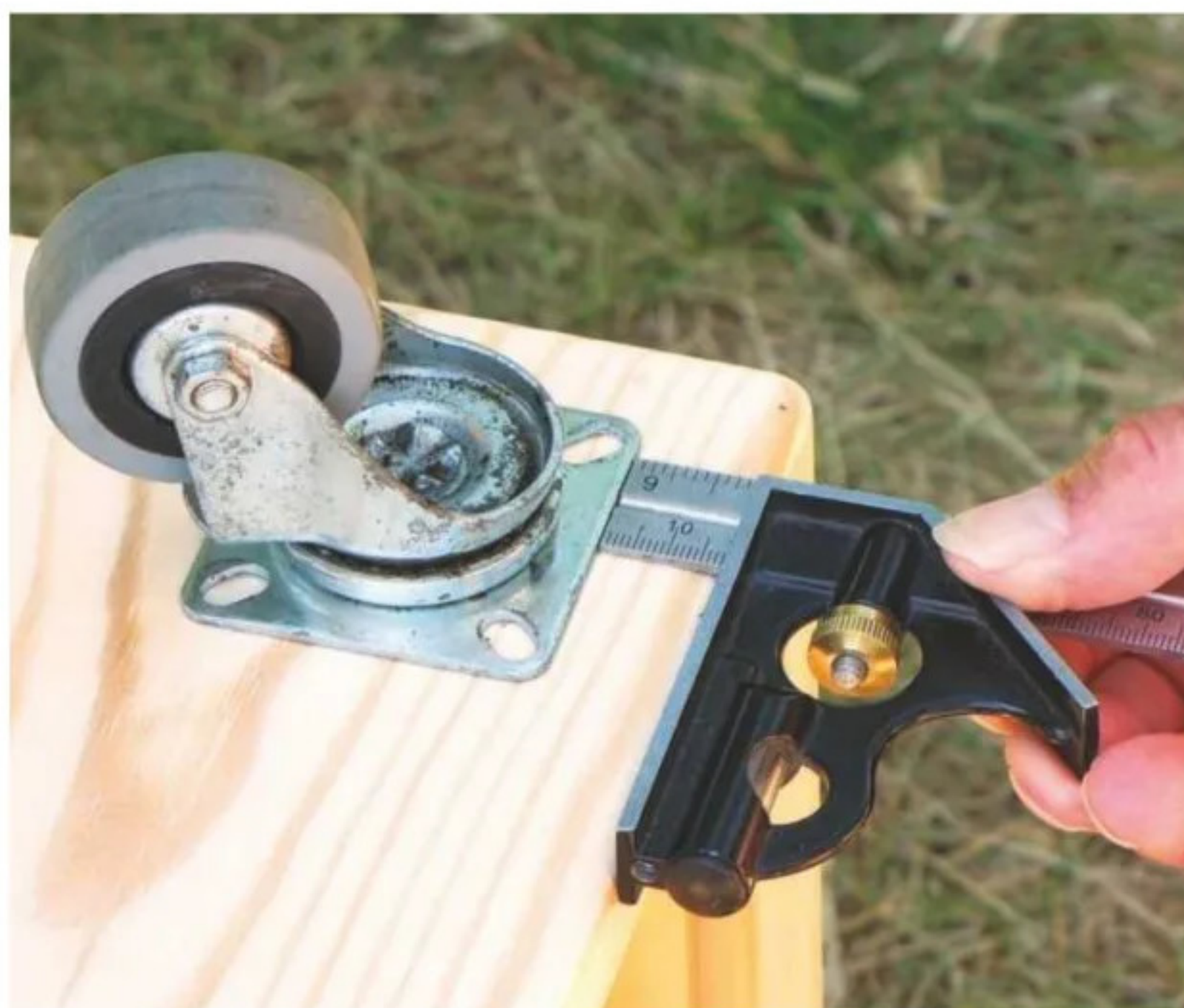
23 Mark the castors' positions and screw to the box. These will be replaced with larger wheels
