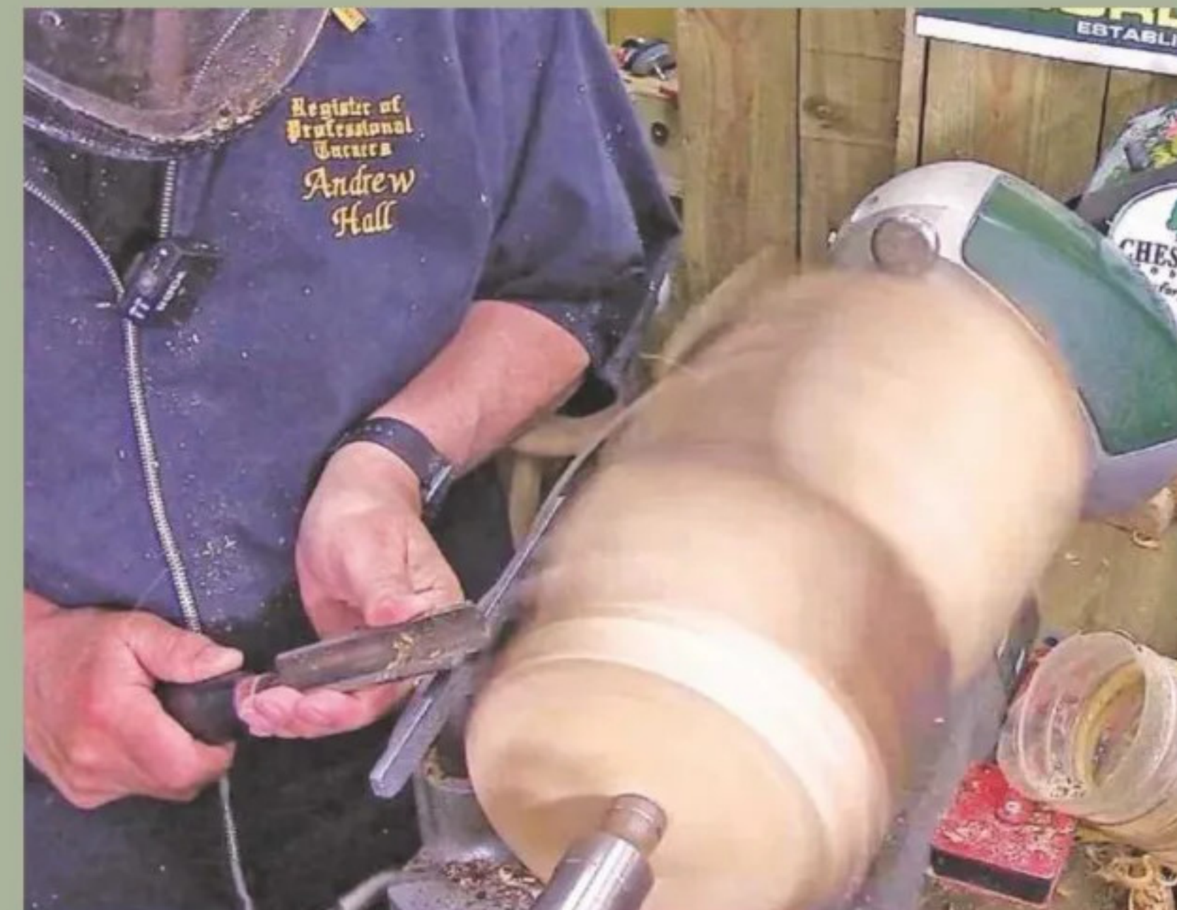
18 Using both the 12mm bowl gouge and spindle roughing gouge, I turn the spindle into a true shape and examine the surface for knots and defects
