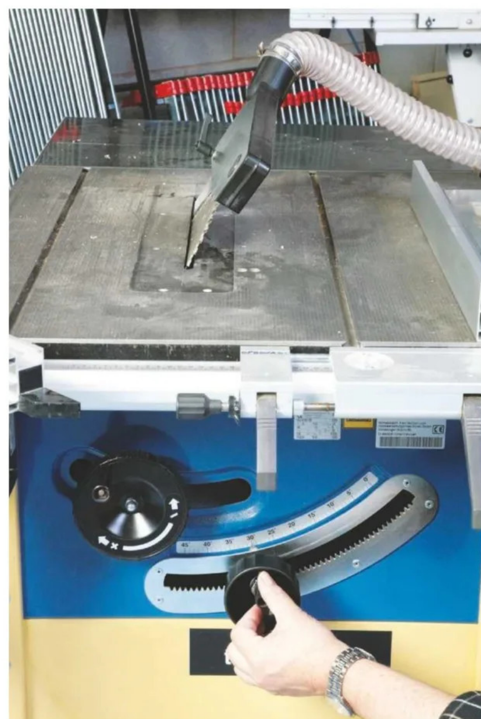
7 The whole rotating mechanism is mounted on a swivel bracket, allowing it to be tilted up to 45° for mitred cuts
