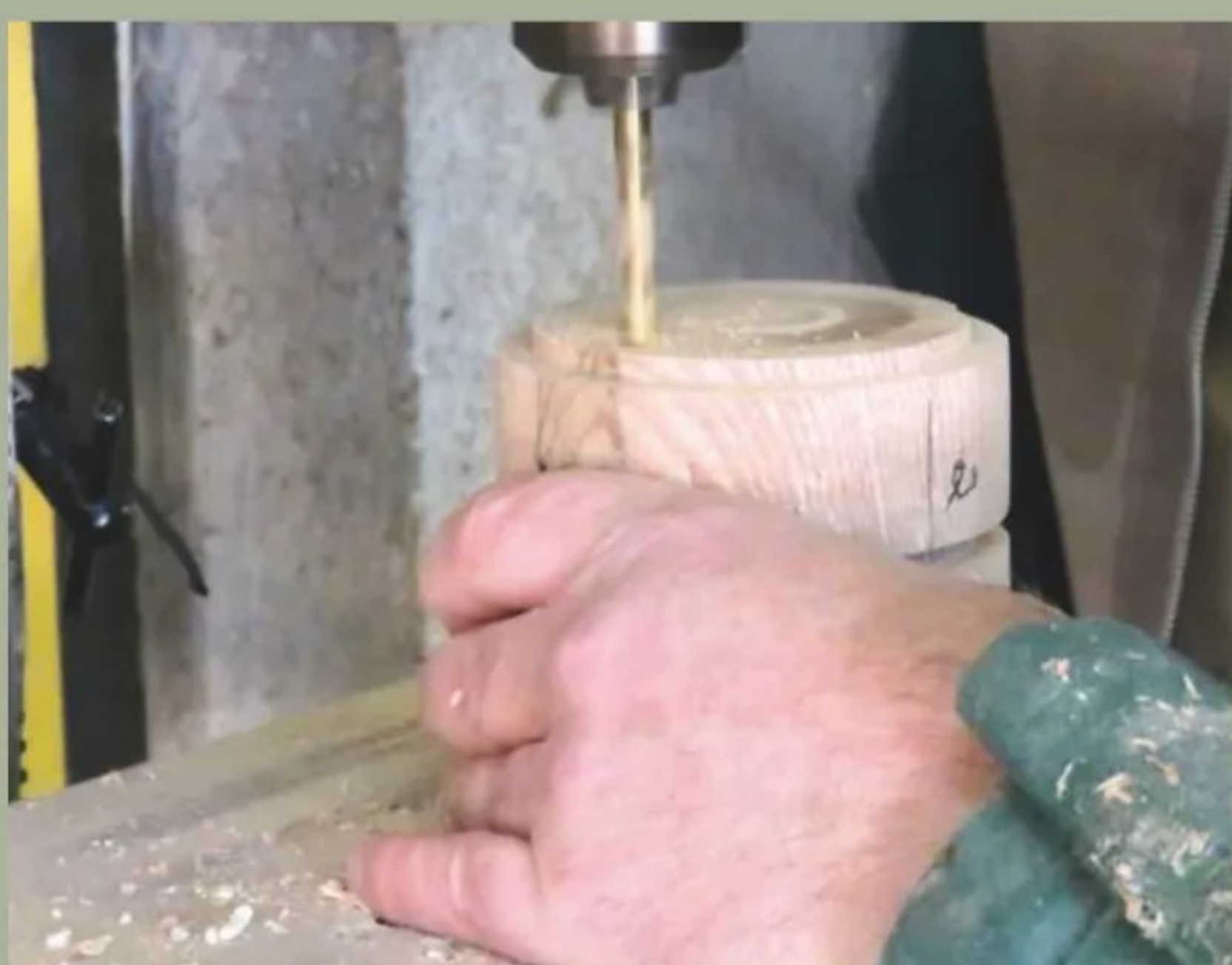
9 Back at the pillar drill, continue to make a hole in the middle tier
