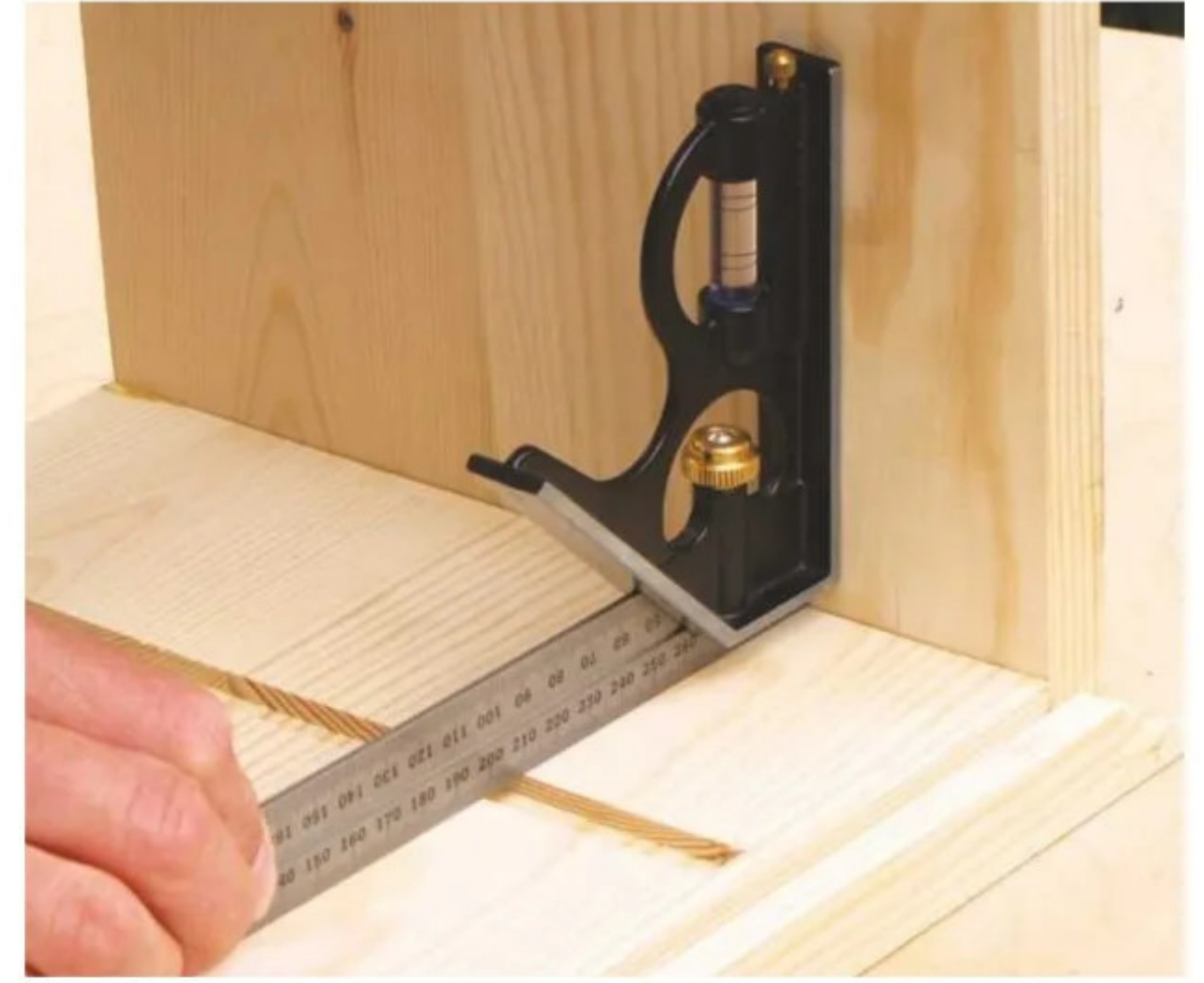
15 Check that everything's square before nailing the joints, adjusting clamps if required
