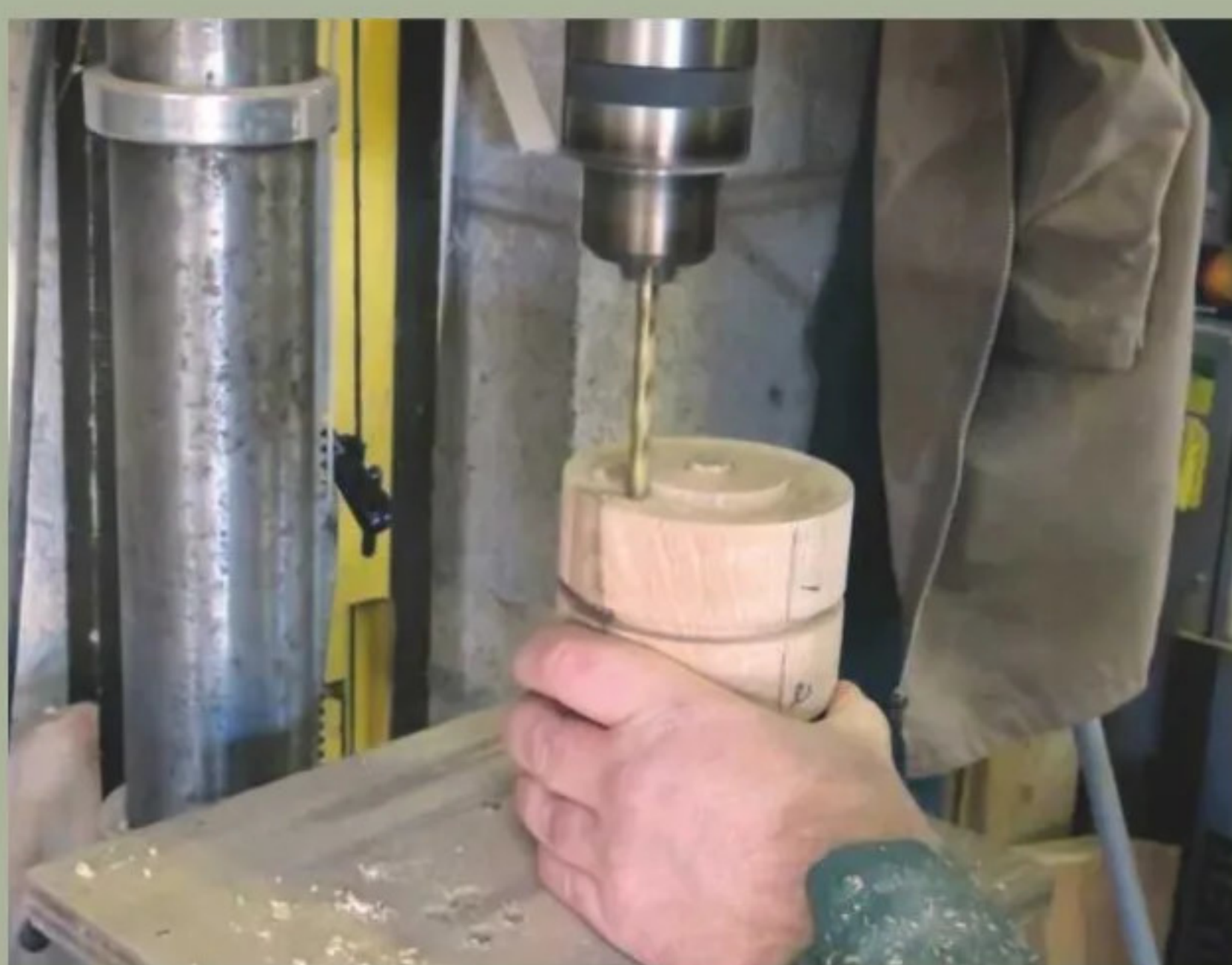
6 Drill a 6mm hole in the base, ensuring it's deep enough to mark the middle tier
