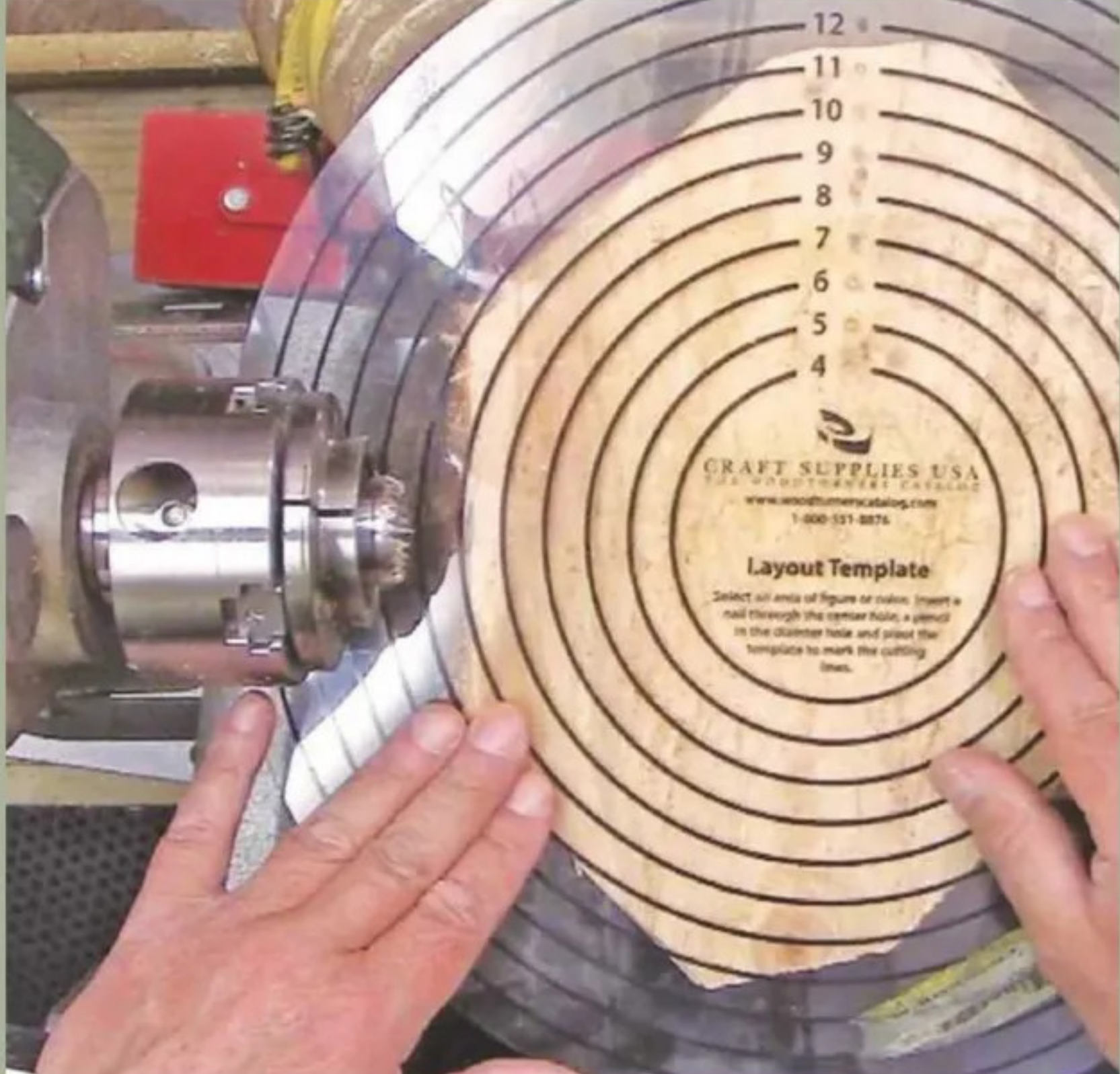
5 To begin, I found the blank's centre using my Craft Supplies USA Layout Template. Available from Lakeland Plastics, they're actually designed for determining cake diameters, and do exactly the same job on turning blanks
