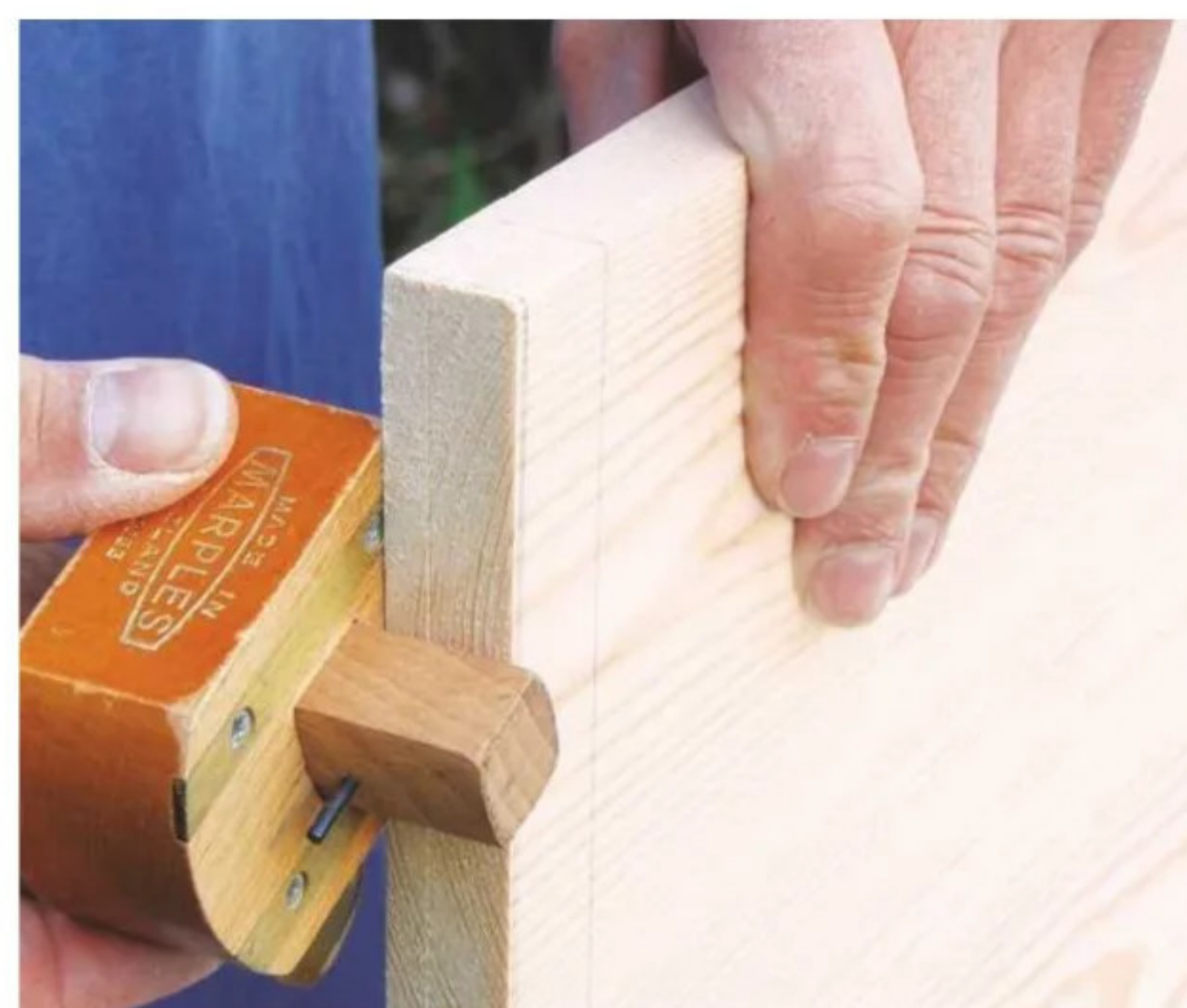
6 Set a gauge to one third of the timber thickness and mark the ends for lap joints. Pencil in the waste
