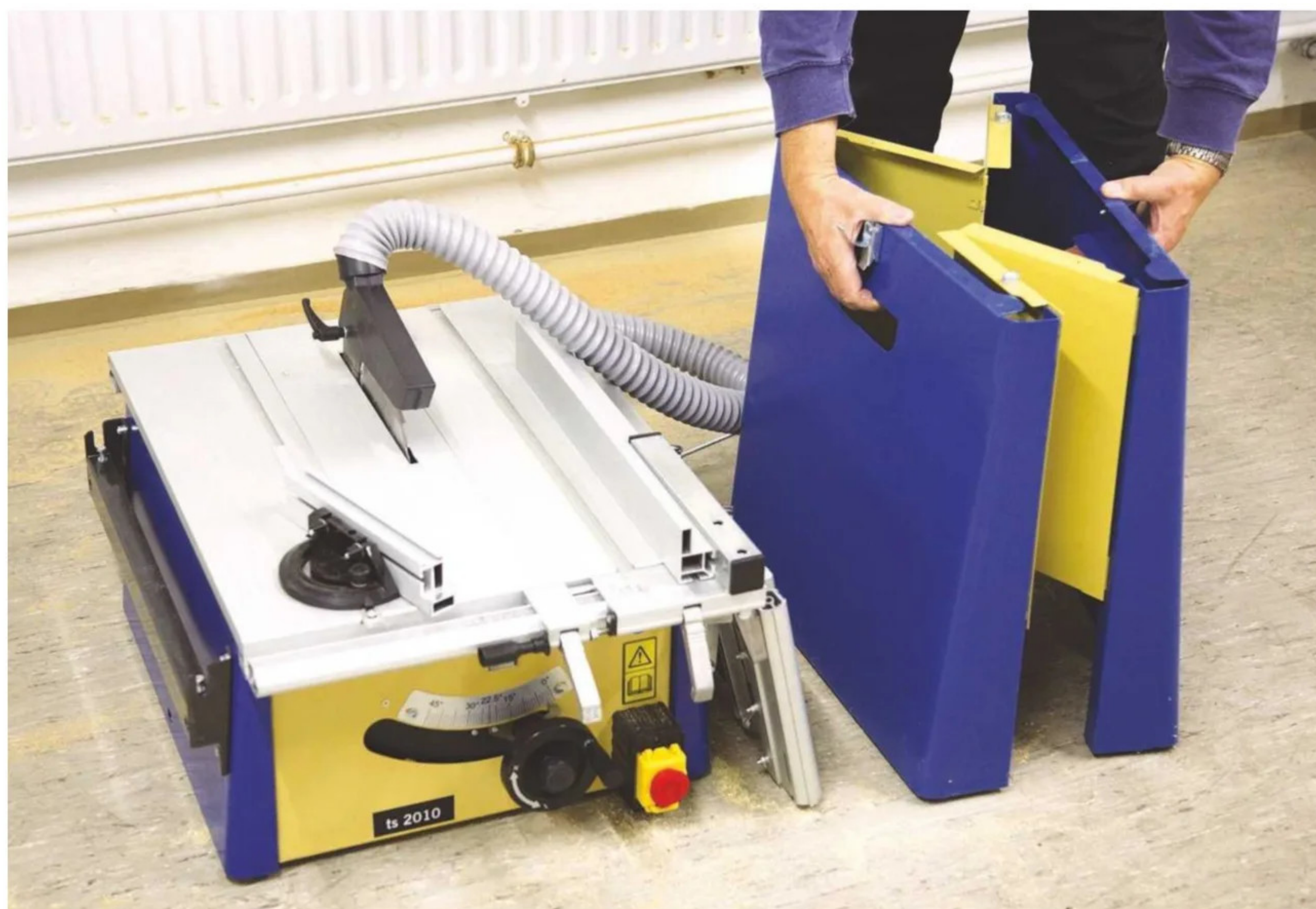
9 A folding stand allows this small cabinet saw to be carried in pieces by one person and taken in the boot of a car
