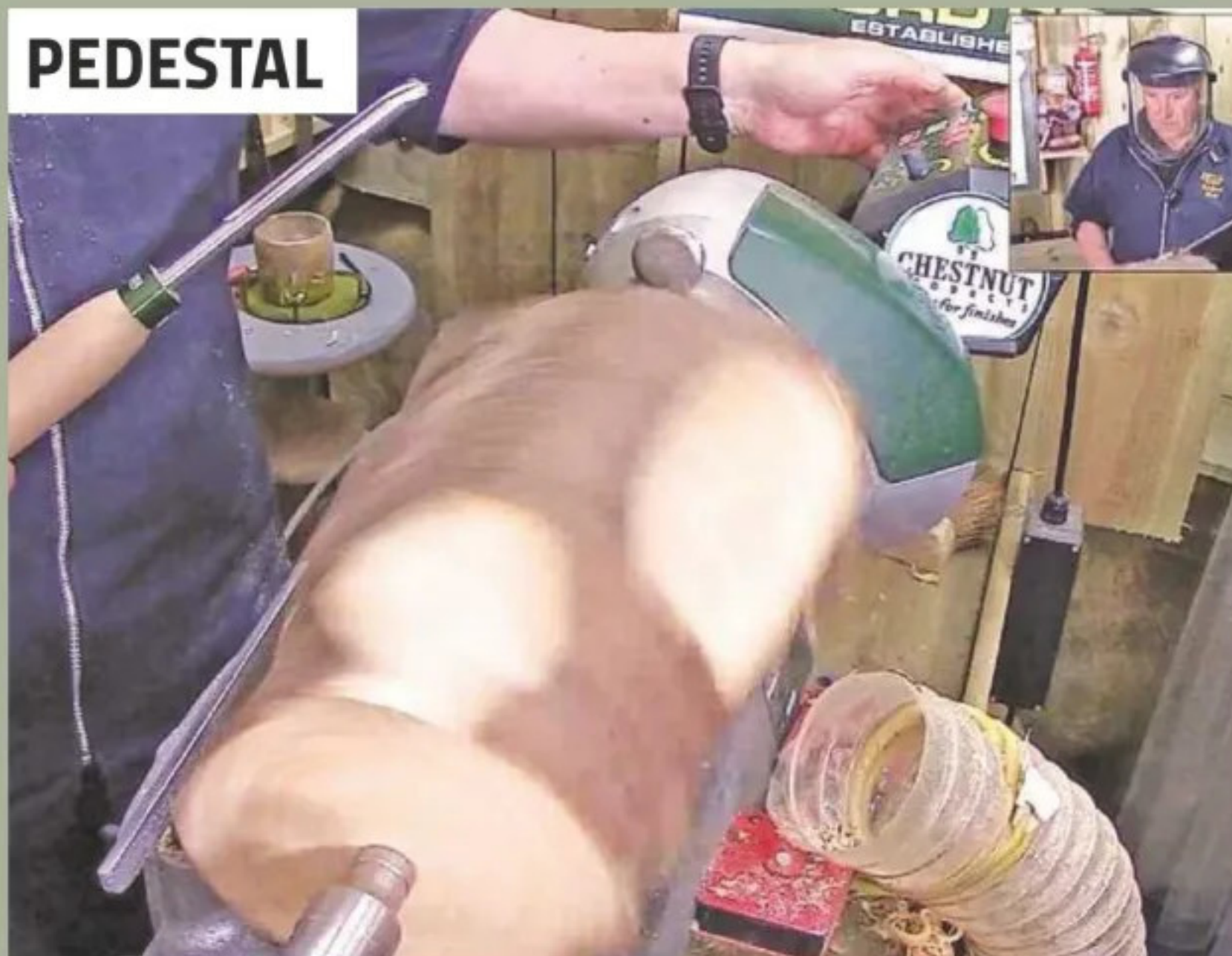
17 Moving on to the pedestal, I mounted the material between centres using the new Record Power multi-tooth sprung point drive centres, which are very useful for spindle turning. I'm looking to remove wood, then try the tenon in the bowl's recess, and if necessary, replace back between centres in order to fine-tune the pedestal's profile. Standing to one side and starting at the lowest lathe speed, I safely begin and increase the rpm until it's running as fast as possible without causing any vibration. As the torque required isn't as great in comparison to bowl turning, I've now moved the belt to the middle position
