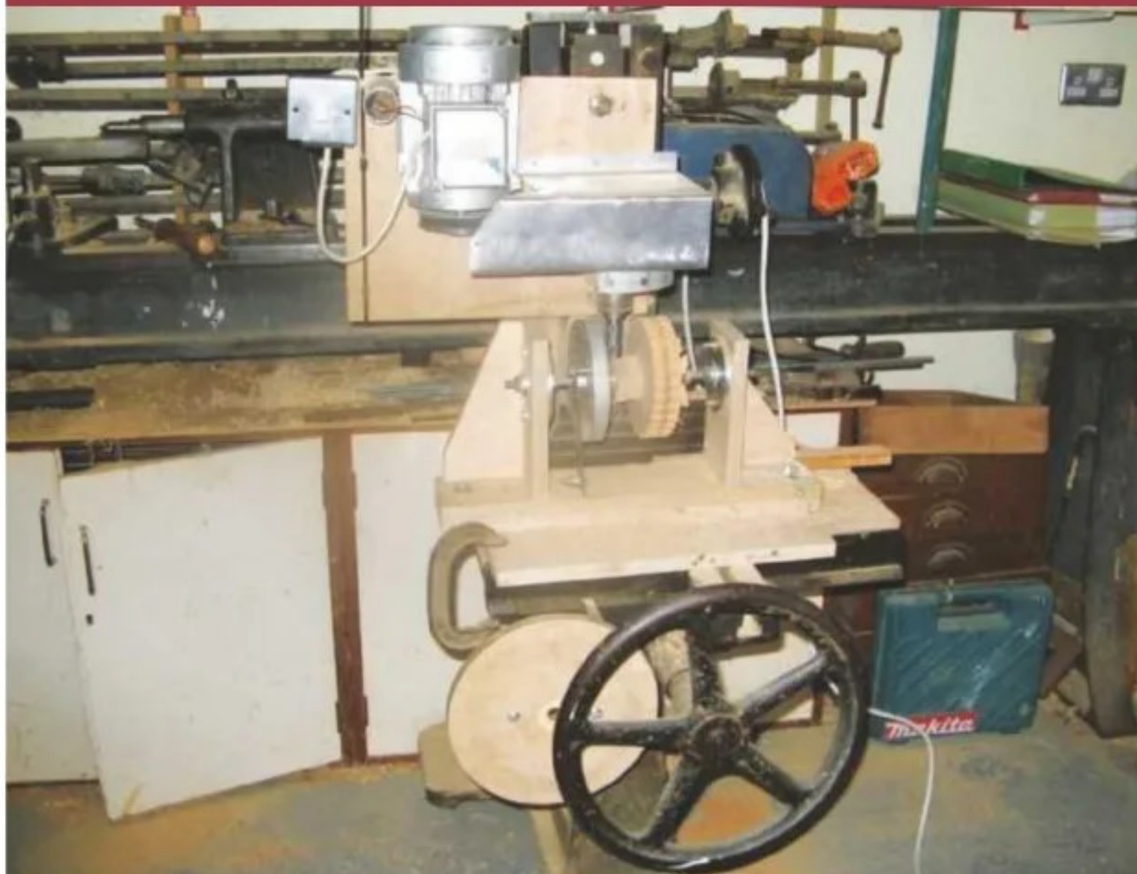
Homemade jig made to turn offset on the cotter pin
