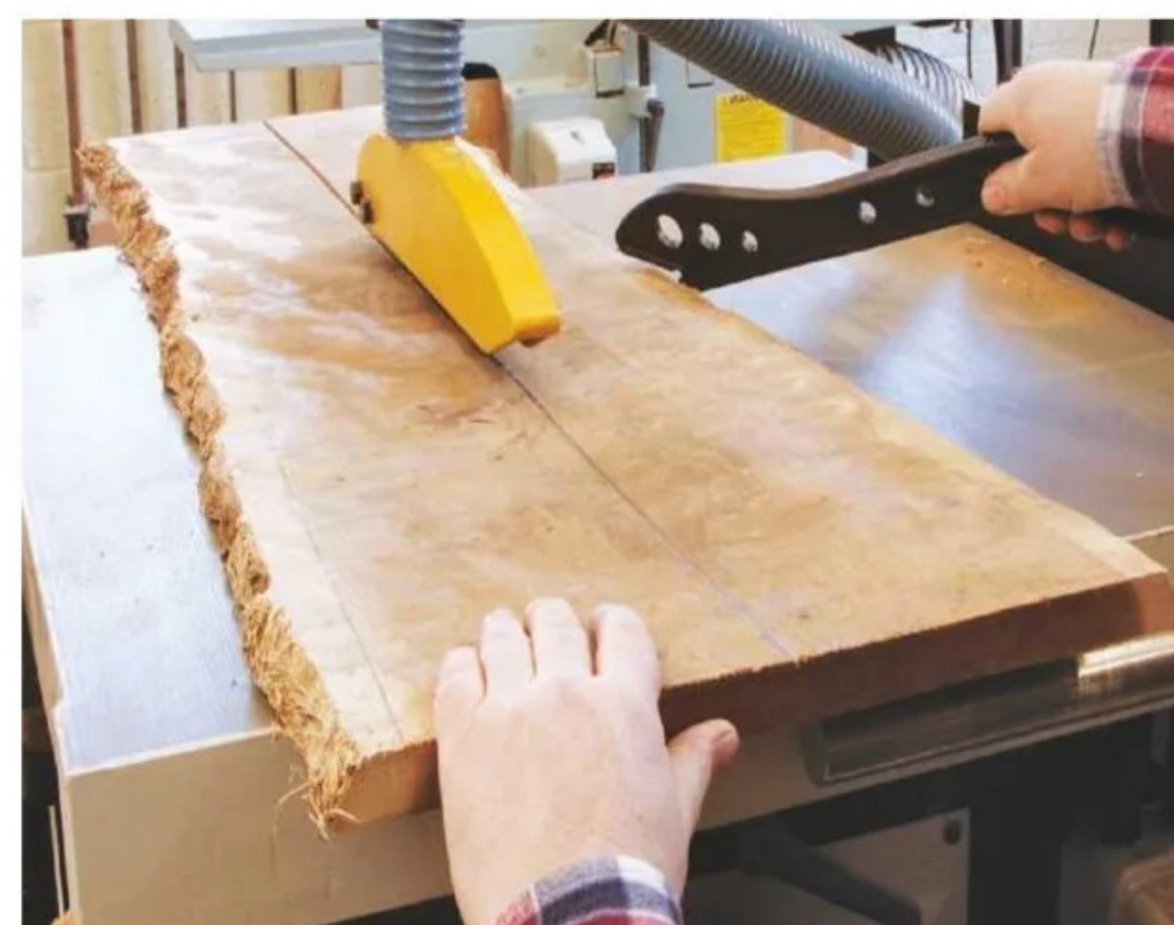
4 Rip-sawing down the board's centreline
