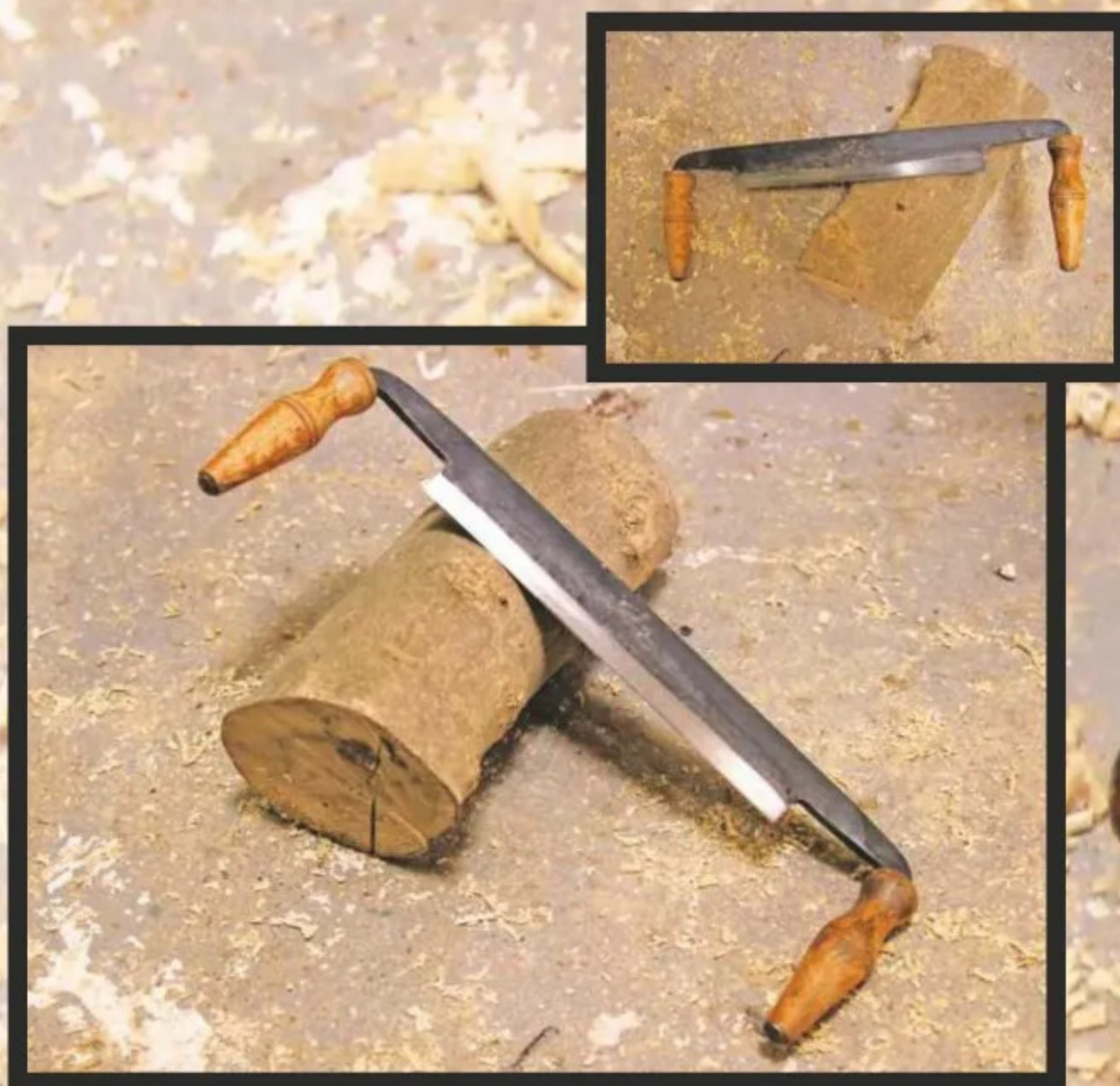
Ashley Iles drawknife – this tool's old quality steel holds a keen edge long after honing
