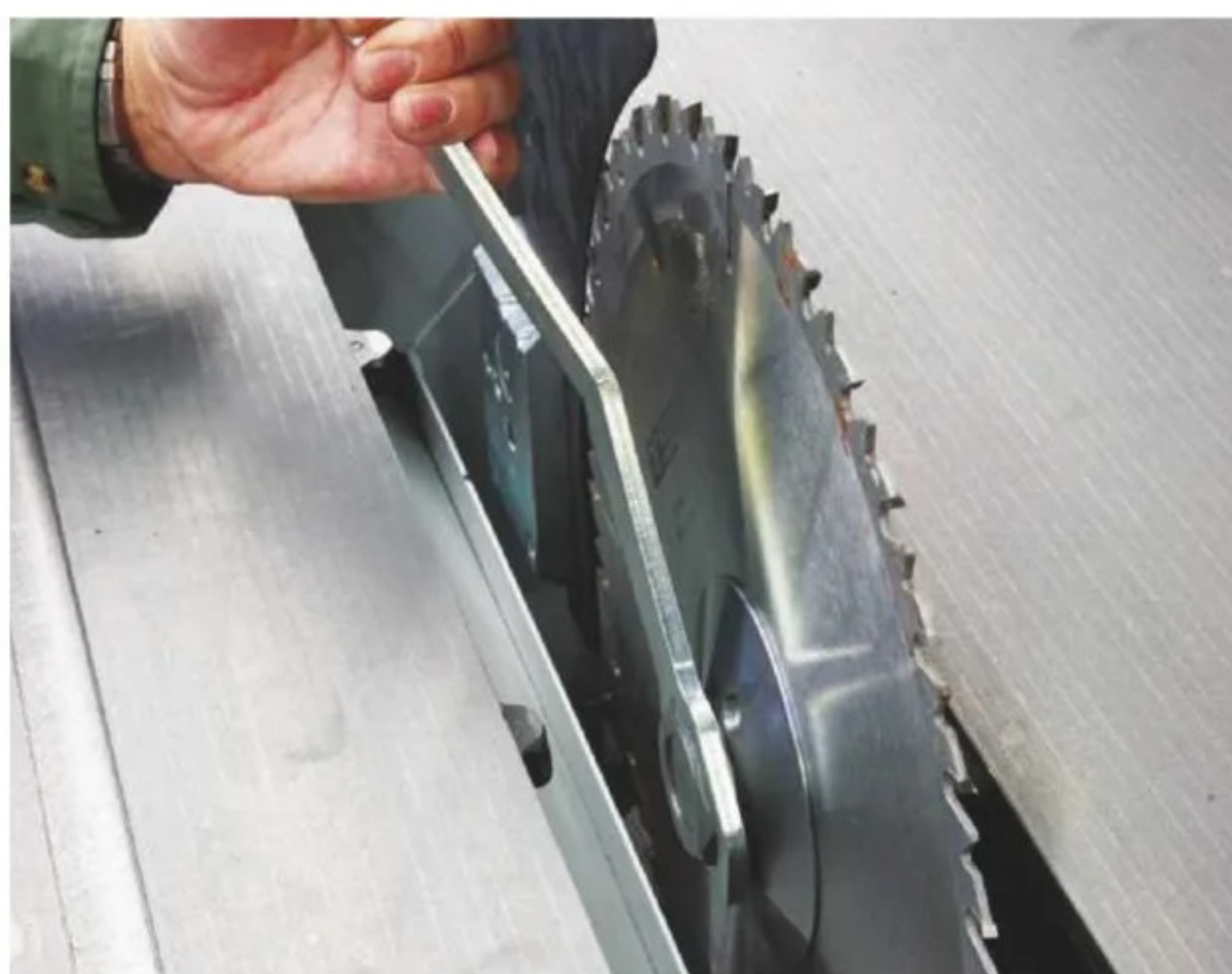
5 When changing a blade, the rotating arbor is locked in place and the securing nut removed
