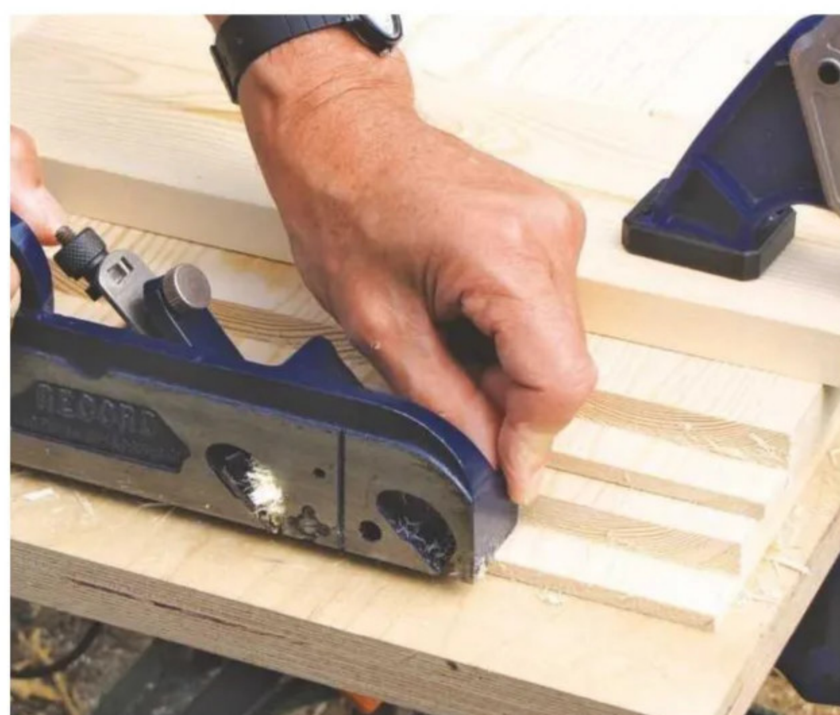
8 If necessary, carefully clean up rebates with a finely-set shoulder or rebate plane – it's worth it!
