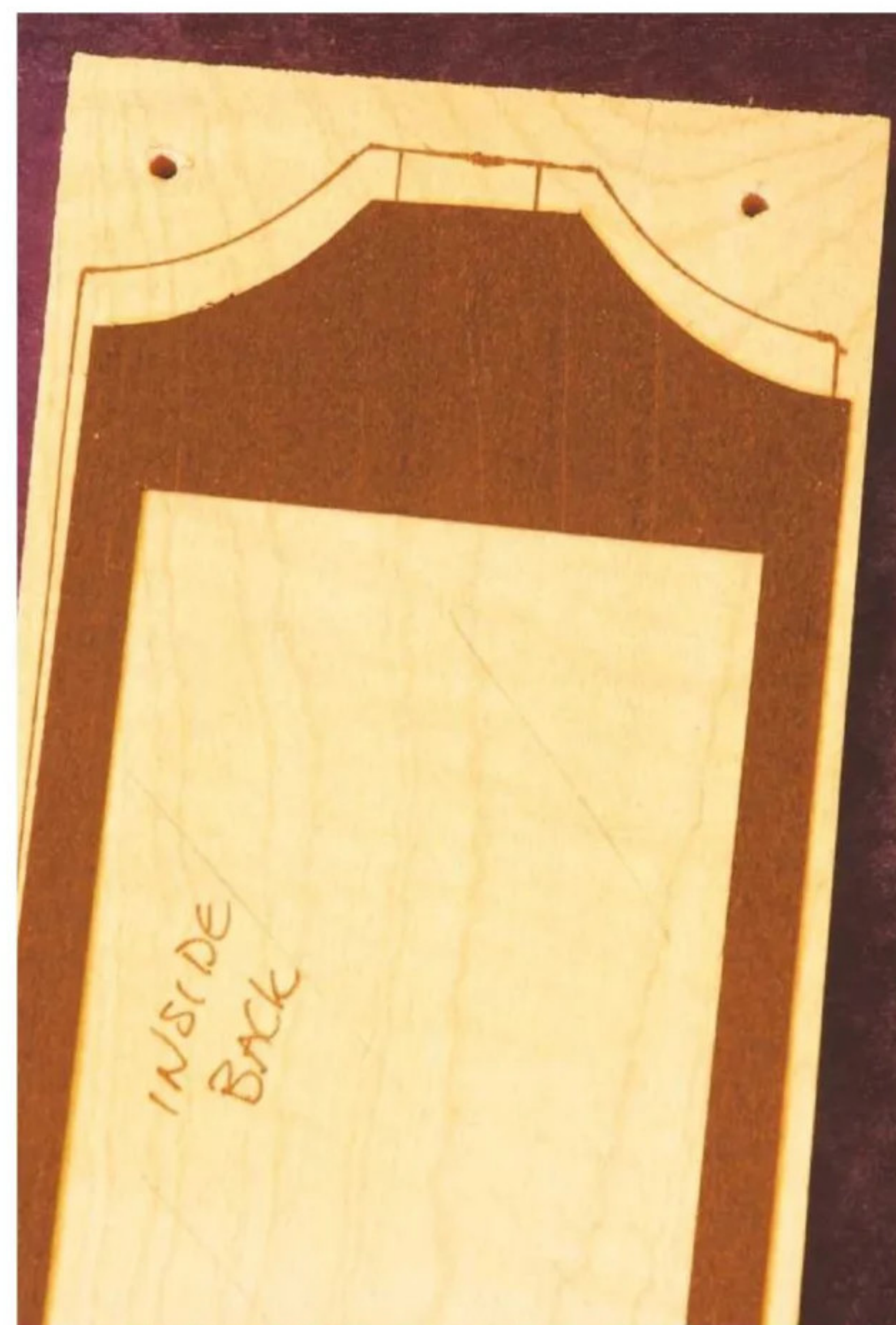
10 Black tulipwood insert between the two soundbox halves
