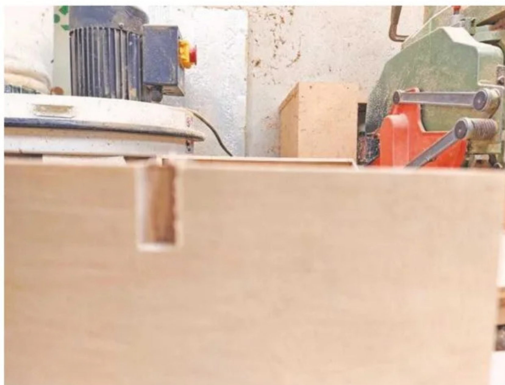
2 Half depth hole drilled into shelf underside
