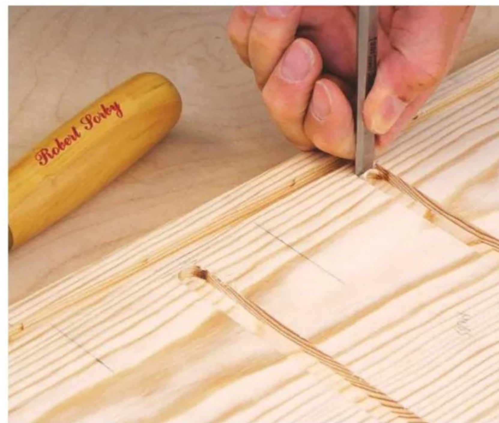
12 For the front panel, housings are stopped 7mm before the groove. Square up ends with a chisel
