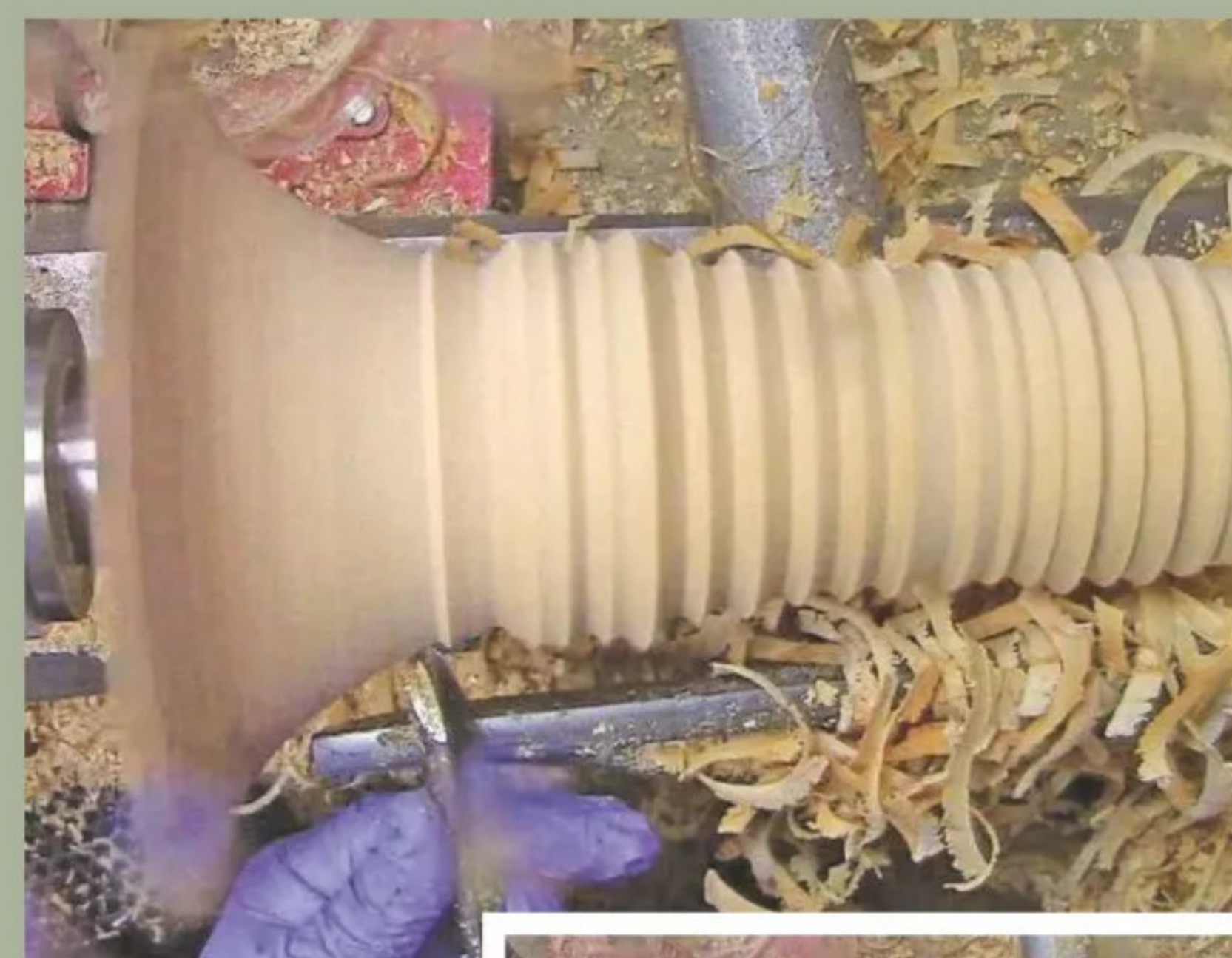
21 Using a series of chisel cuts to reduce the diameter and create a pleasing shape, I cut a bead at the tailstock end onto the spigot; this leaves a nice transition where pedestal meets bowl. This is a great opportunity to practice using the tools for both shape and design purposes
