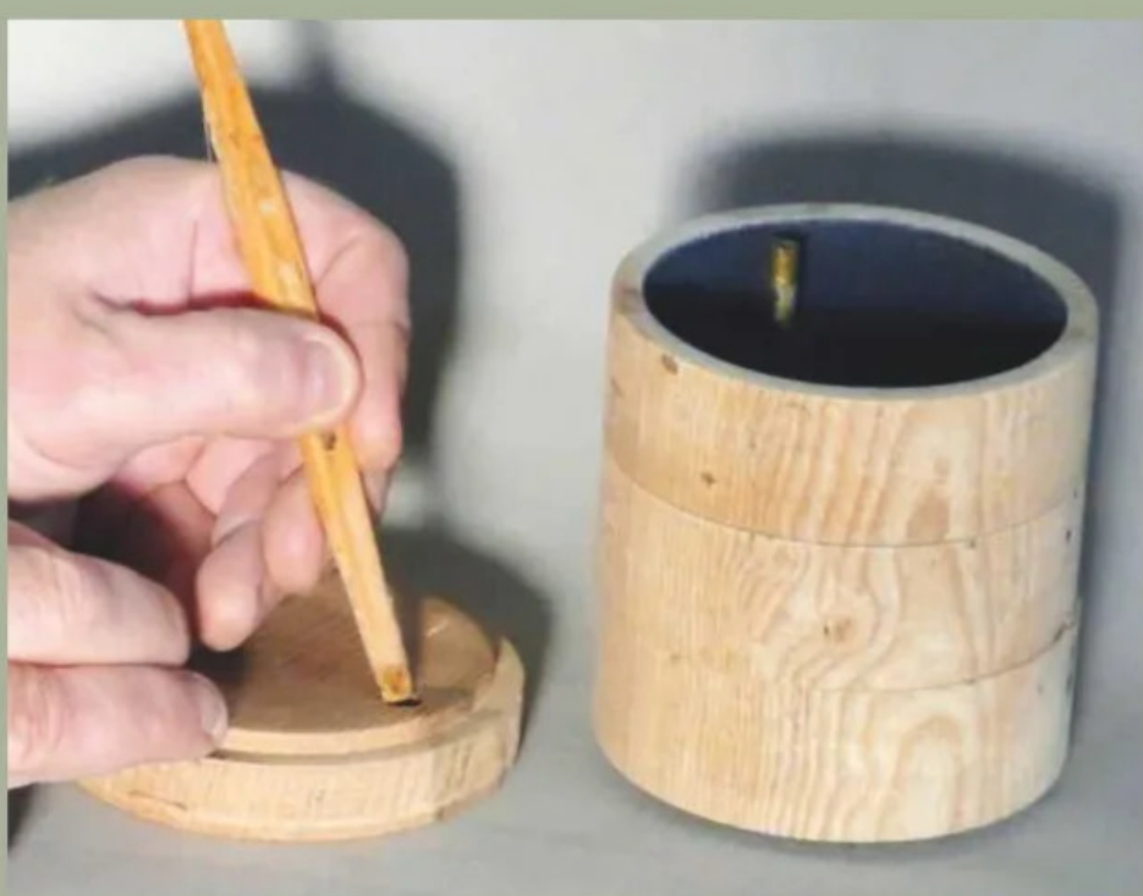
23 Reassemble your box and epoxy the metal rod into the hole previously drilled in the lid
