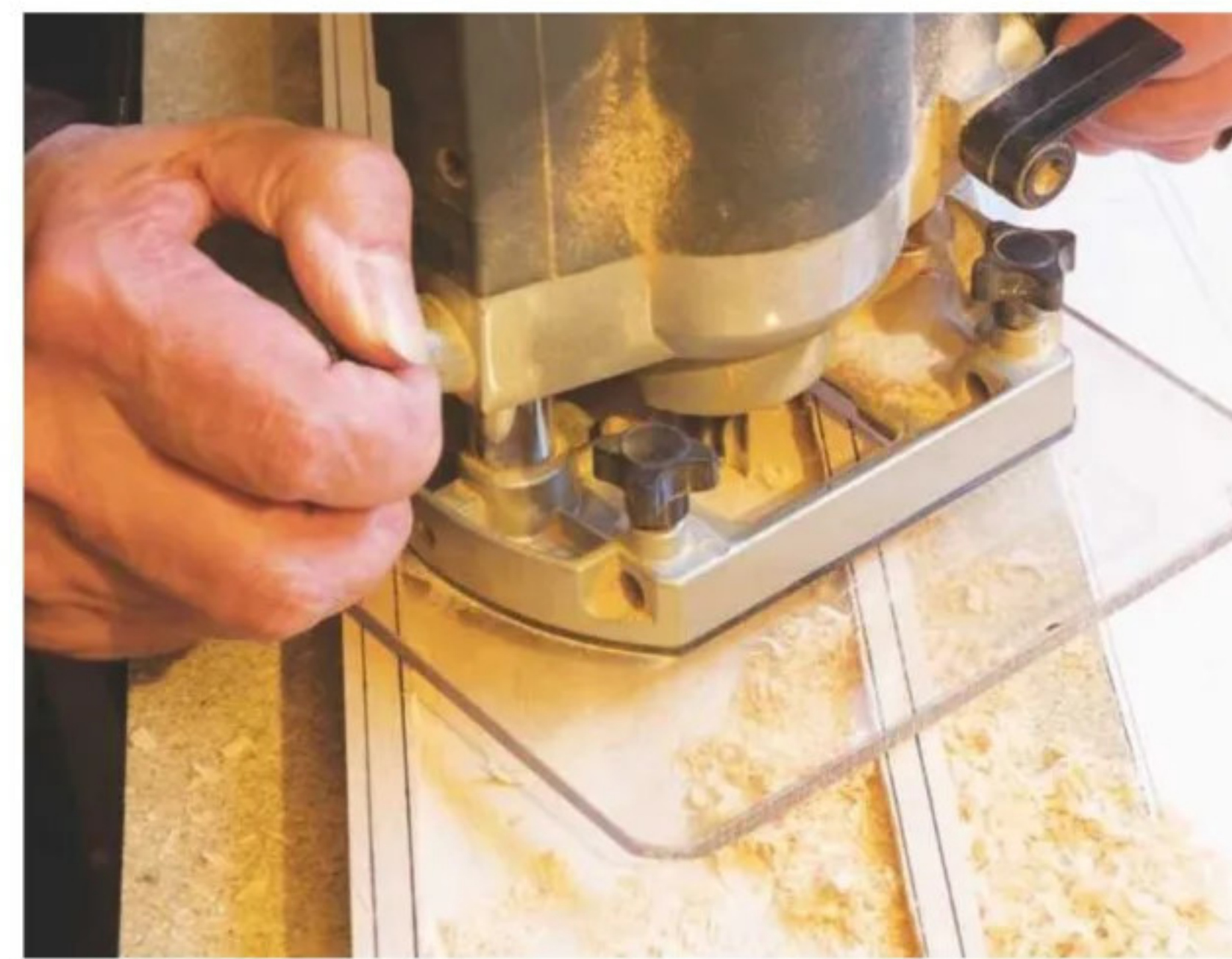
6 Hollowing the soundbox with a router
