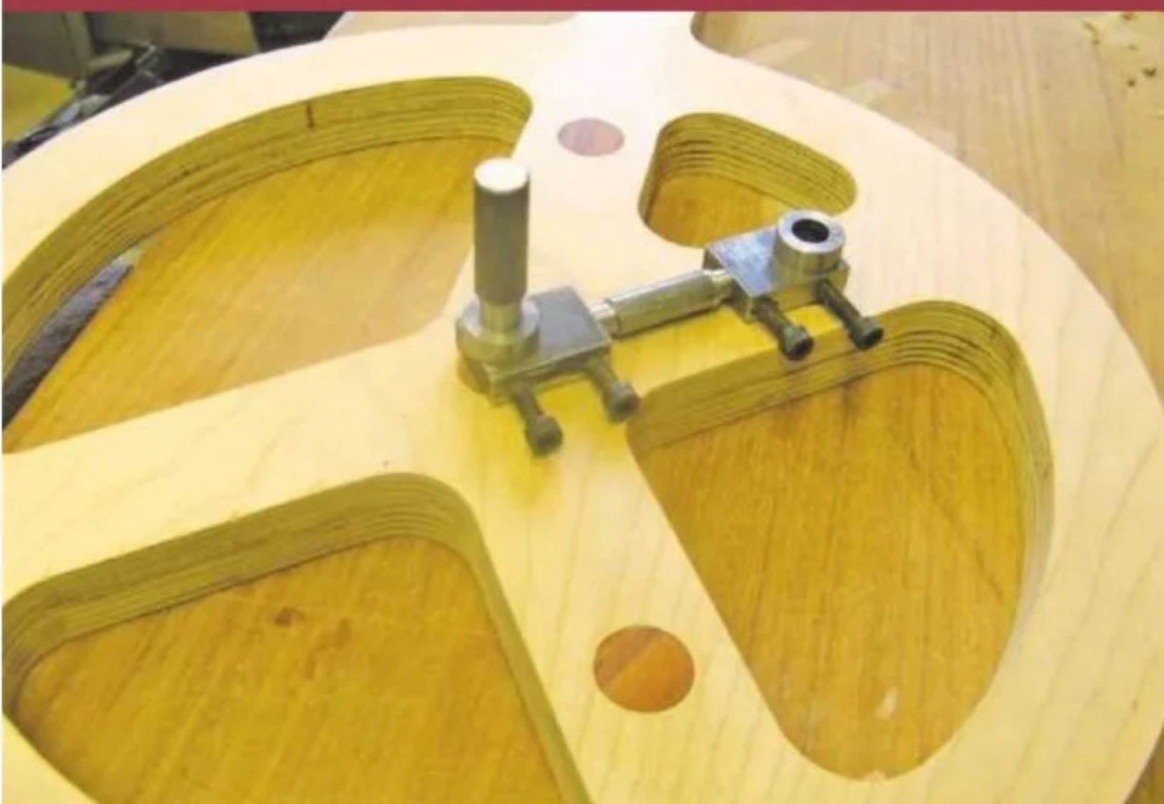
A mild steel pin is inserted into the centre bush; the jig is then located over the next hole to be drilled
