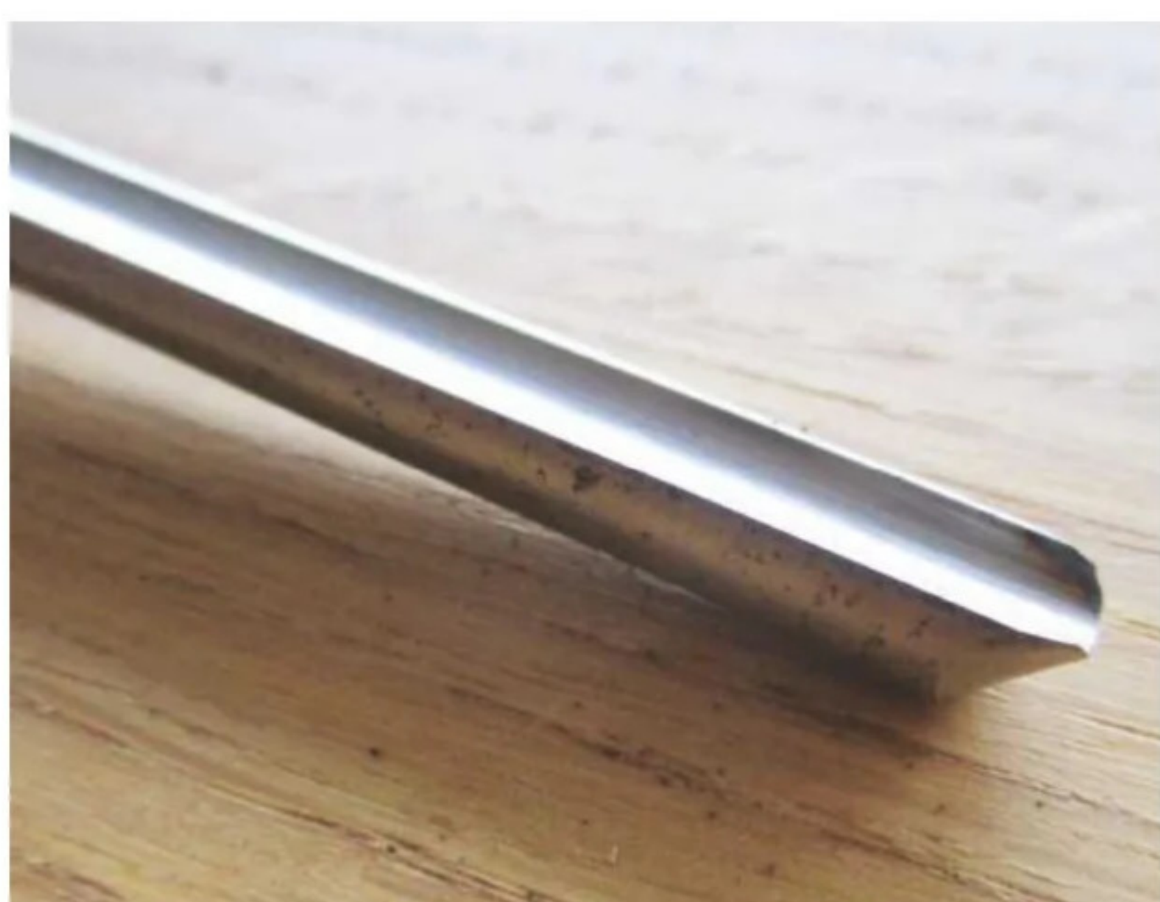
The resulting grind on a spindle gouge looks good
