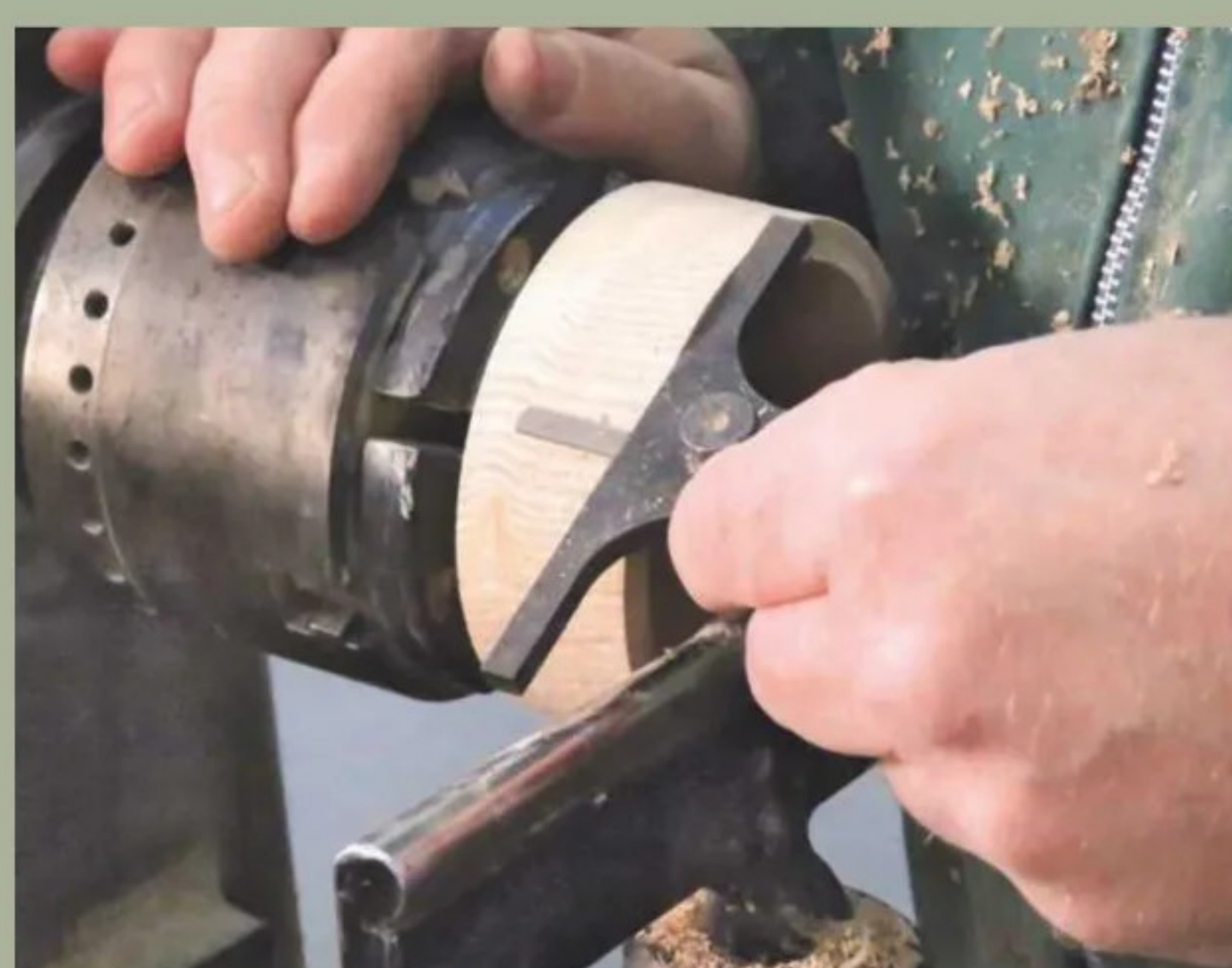
13 You can then check the hollow's depth using a depth gauge
