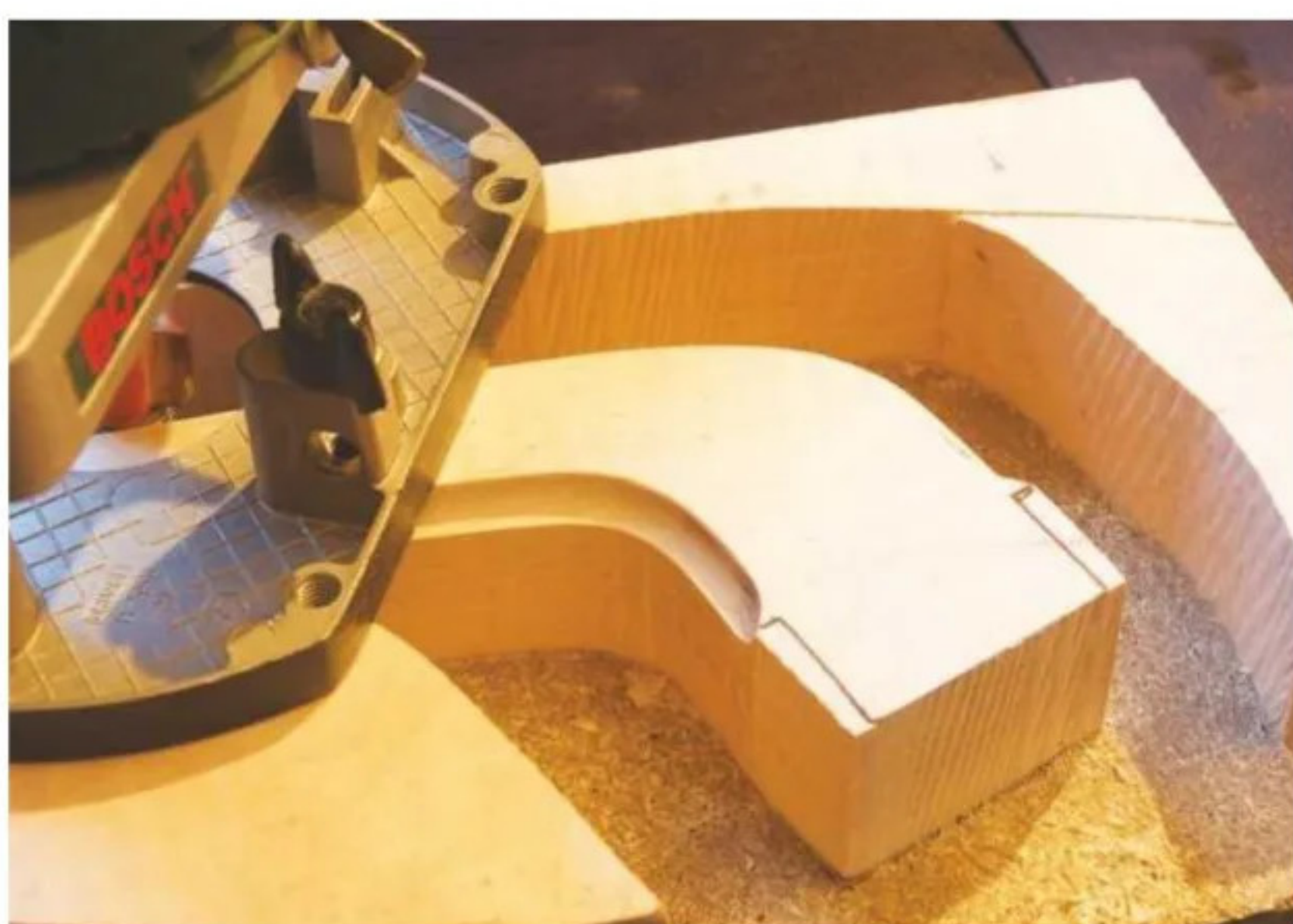
14 Stop just short of the tenon's length
