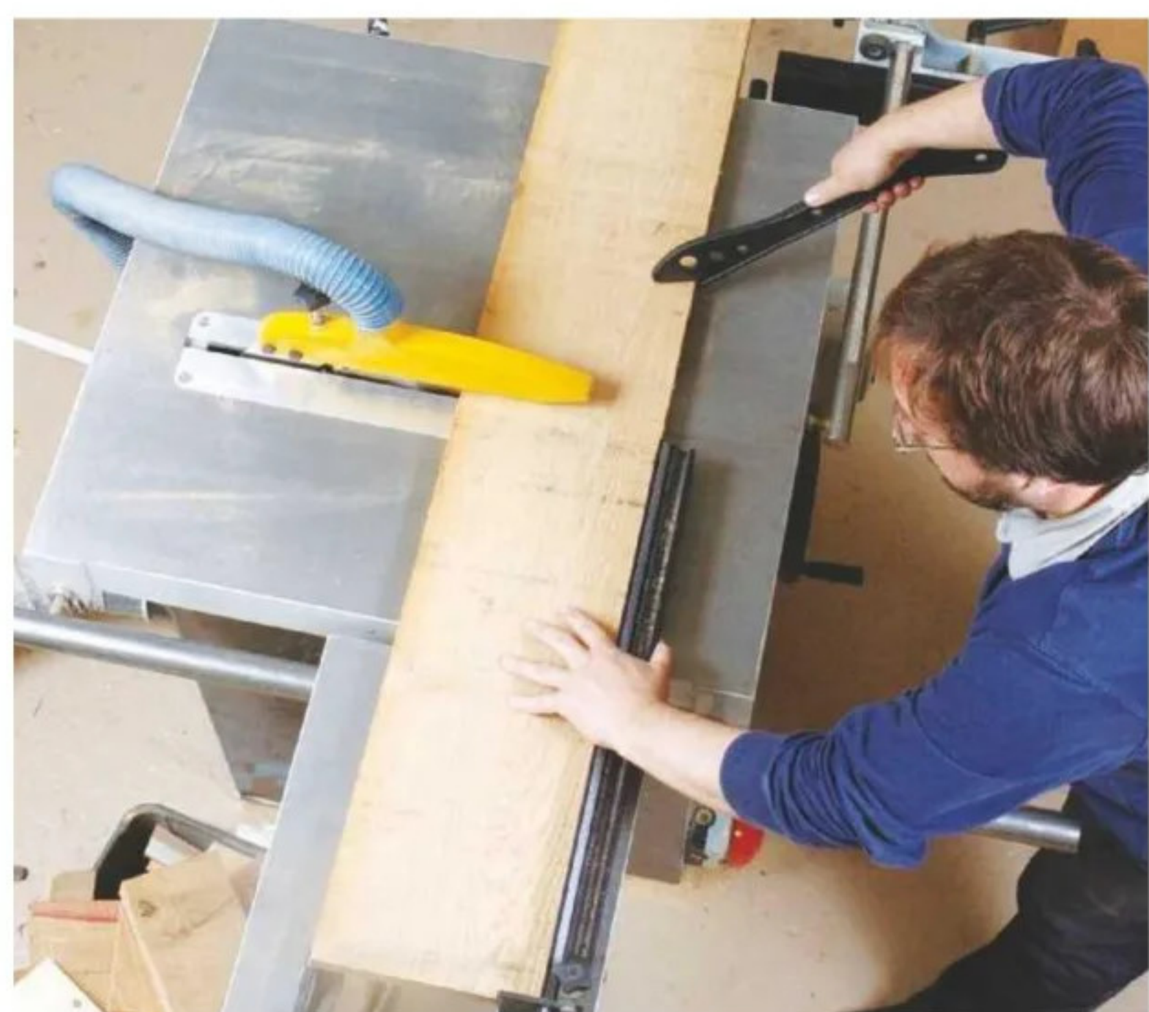
2 Seen from overhead, here I'm cross-cutting a board on the sliding carriage, using a push-stick in my right hand
