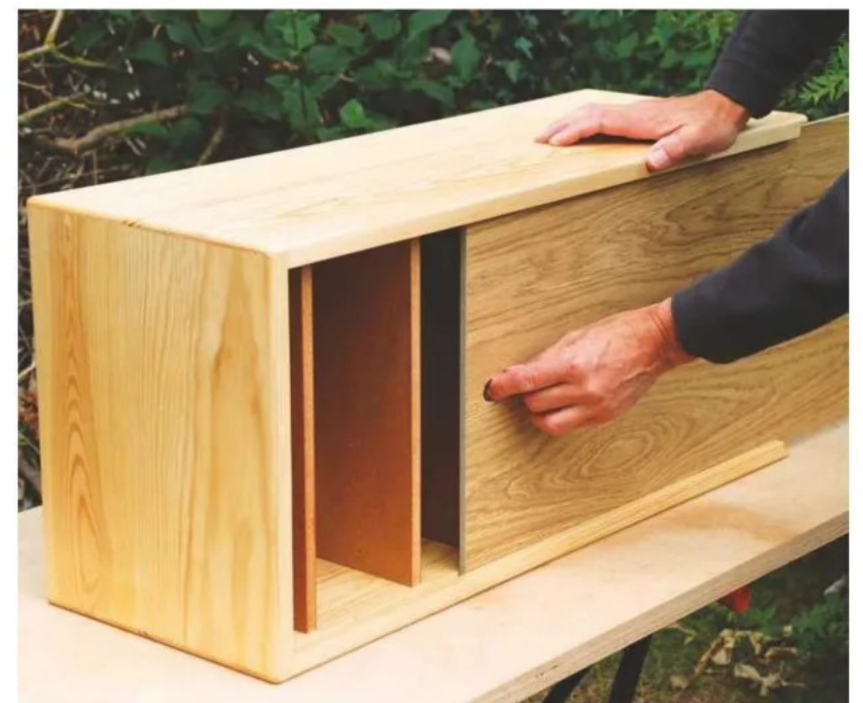
24 Check to ensure the front panel slides properly, then drill a 22mm diameter finger hole ✂
