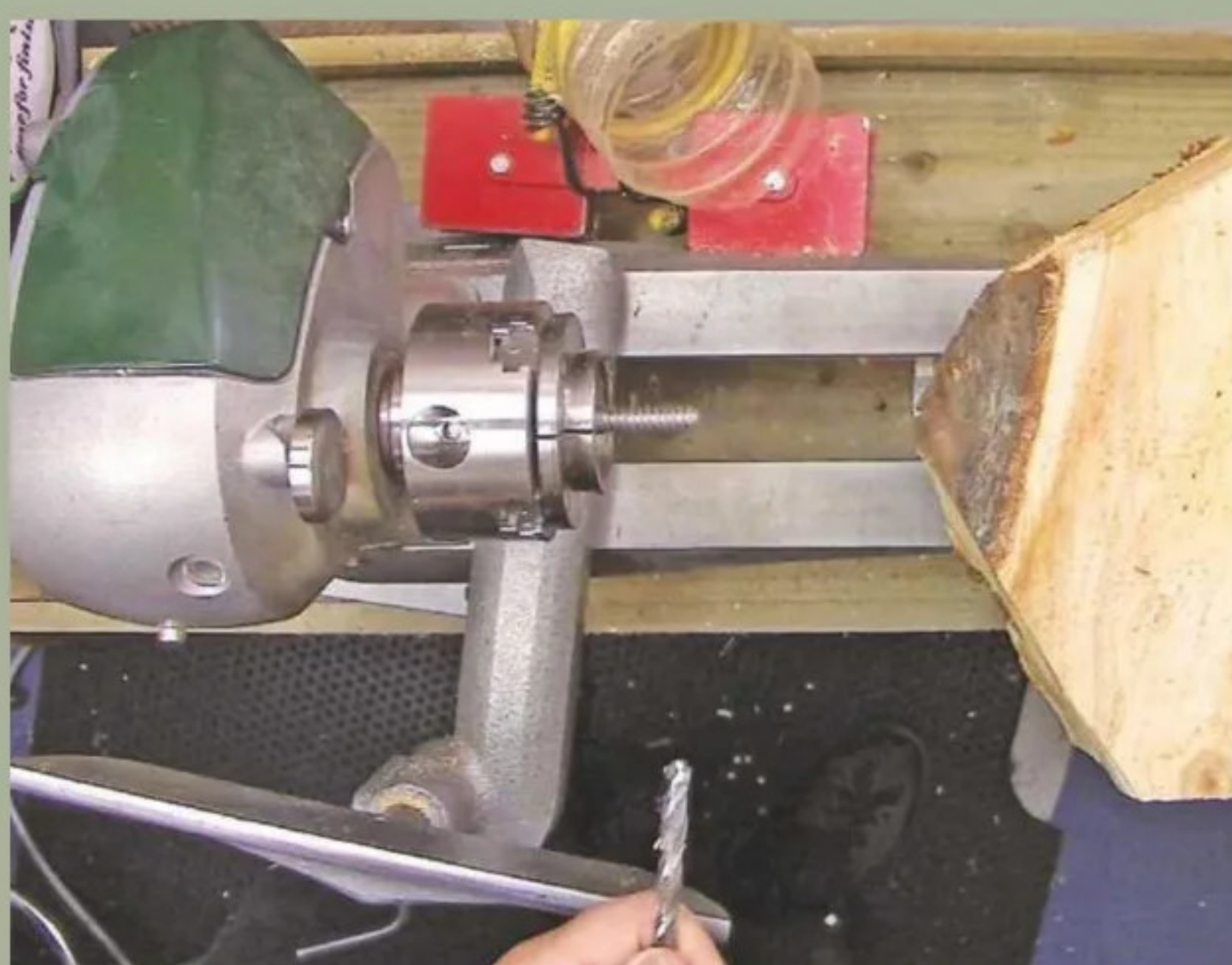
6 I drilled a 7mm hole for a 9mm screw chuck to hold on, with added support from the tailstock
