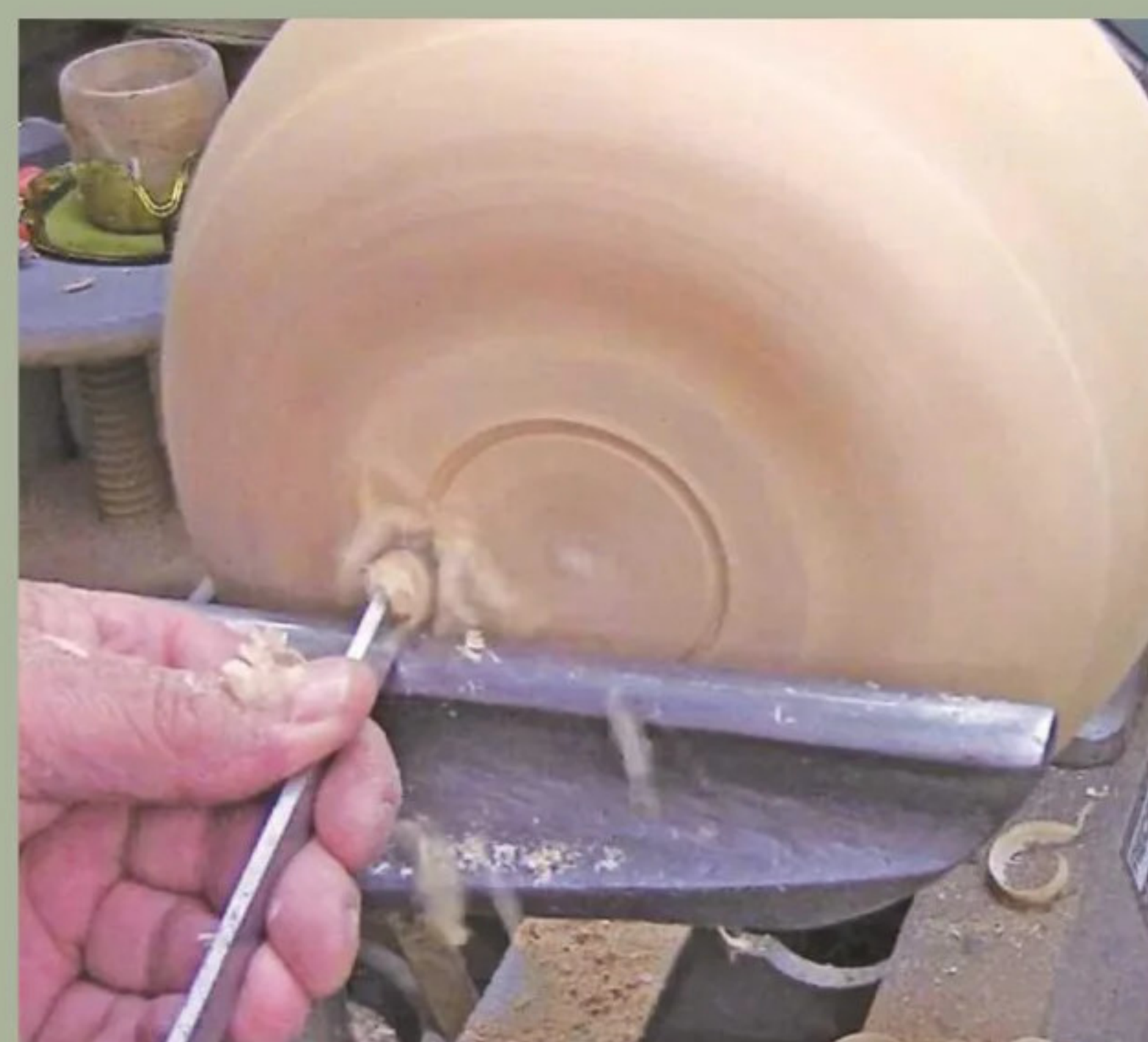
11 Using standard 50mm jaws and a set of dividers, I cut the recess with a 4mm parting tool
