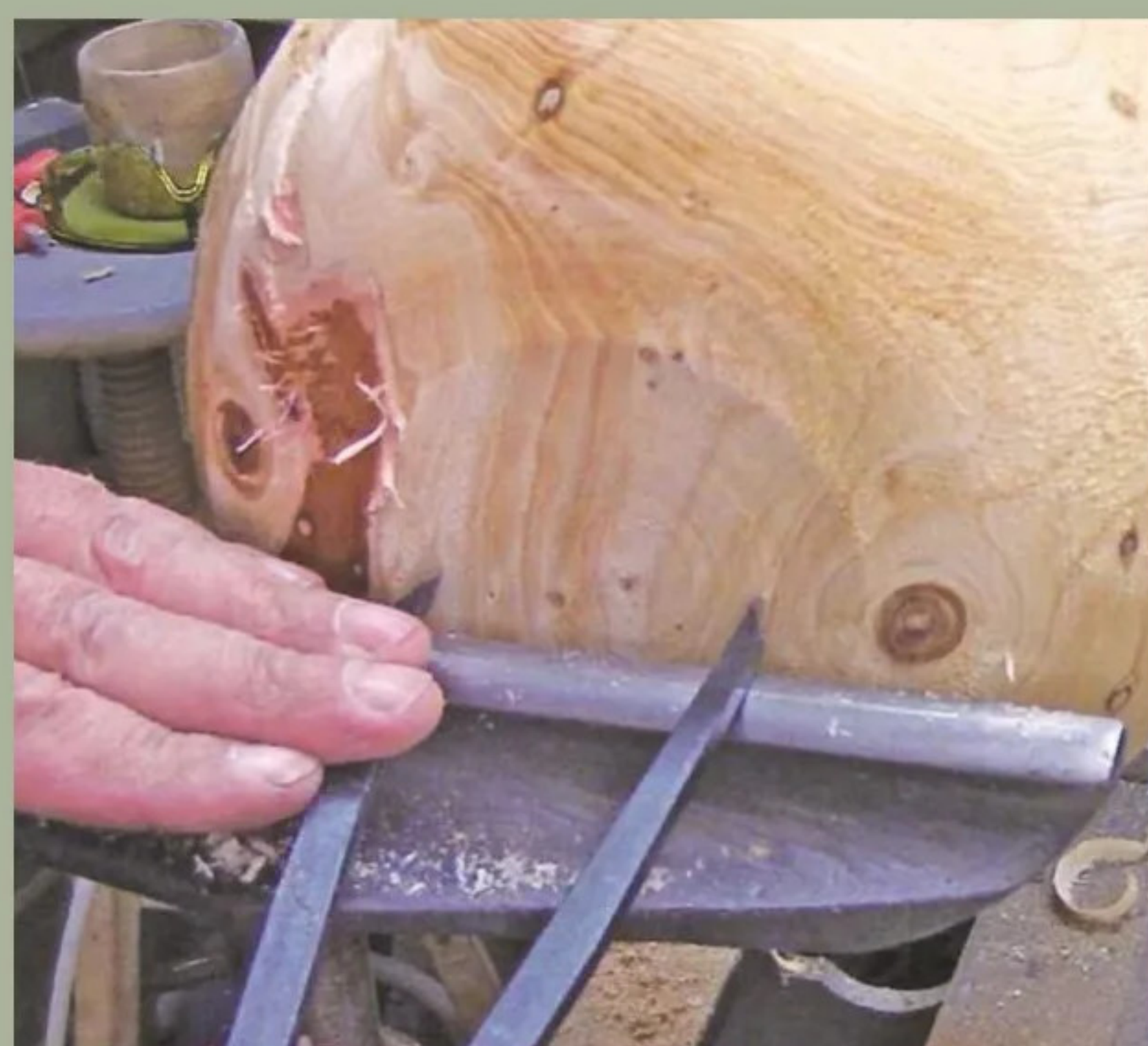
10 After truing up the shape, I measured the pedestal's recess, which needed to be the same size as the optimum circle on my Record Power SC3 chuck
