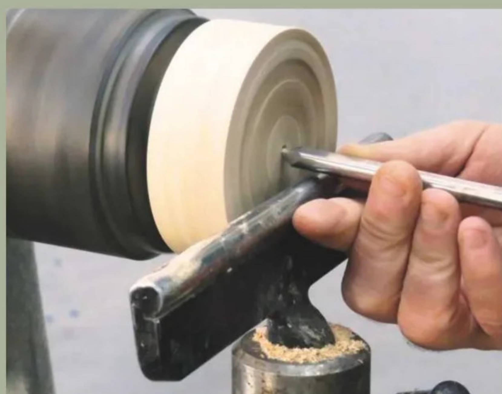
10 Hollow the base by first drilling a hole in the centre with a spindle gouge...
