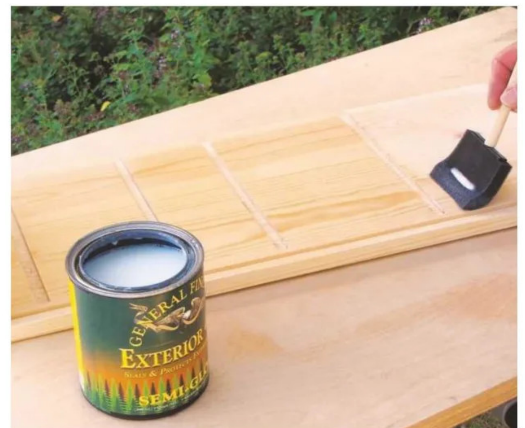
21 Finish the interior with a suitable exterior varnish. Yacht varnish is best for the outside surfaces
