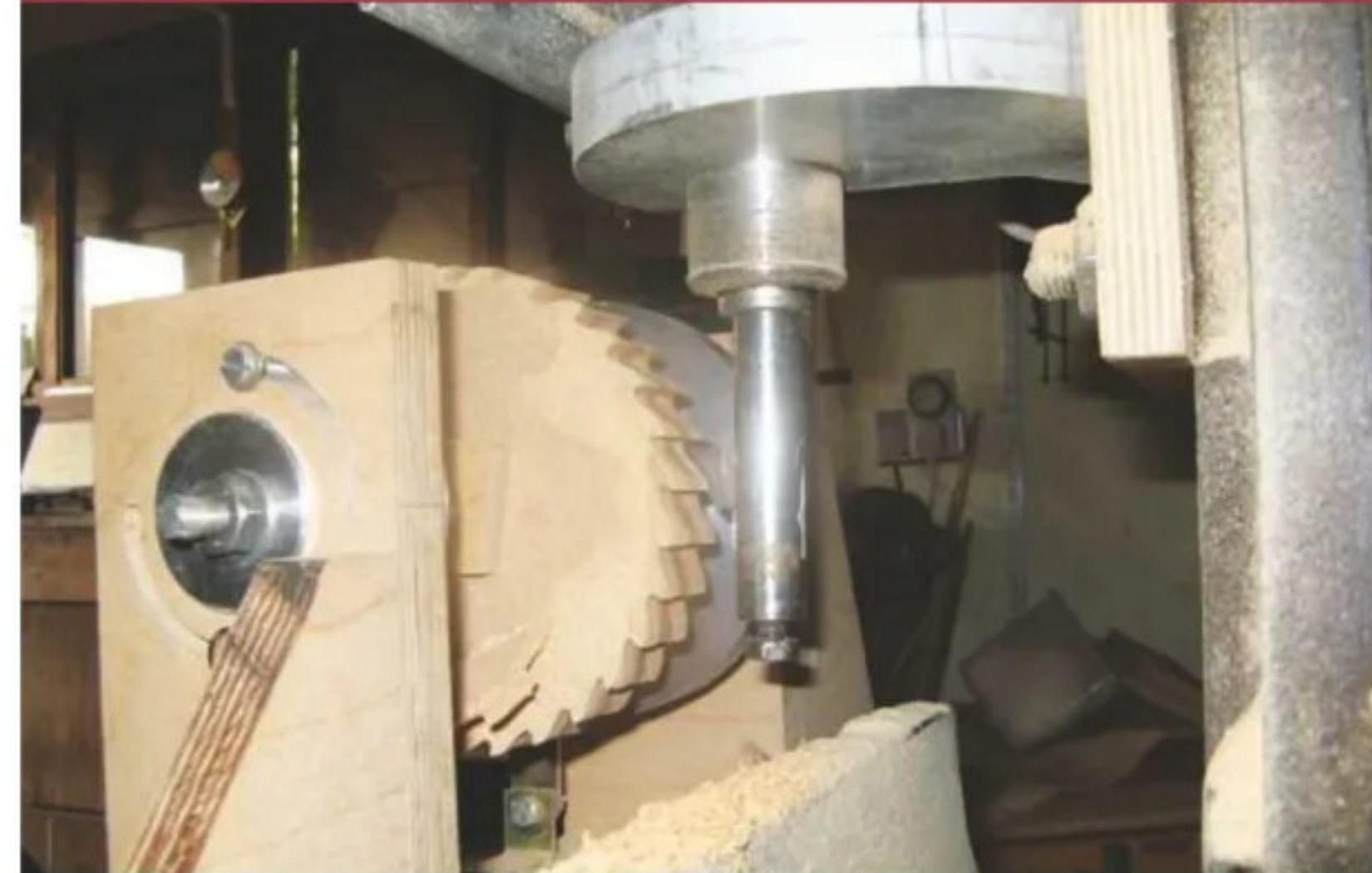
Escape wheel cutting using the homemade inverted French head
