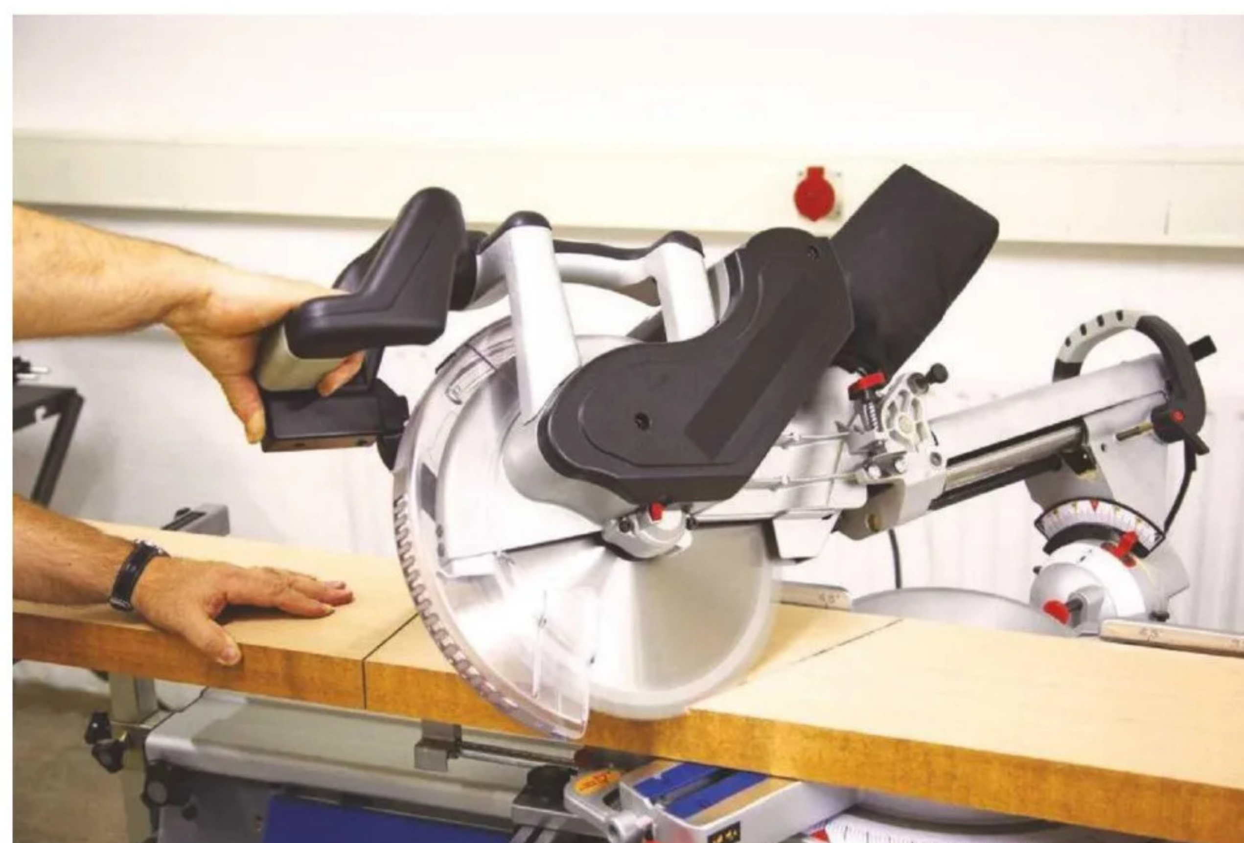
12 An alternative to a saw bench is a high performance cross-cut sliding arm cross-cut saw
