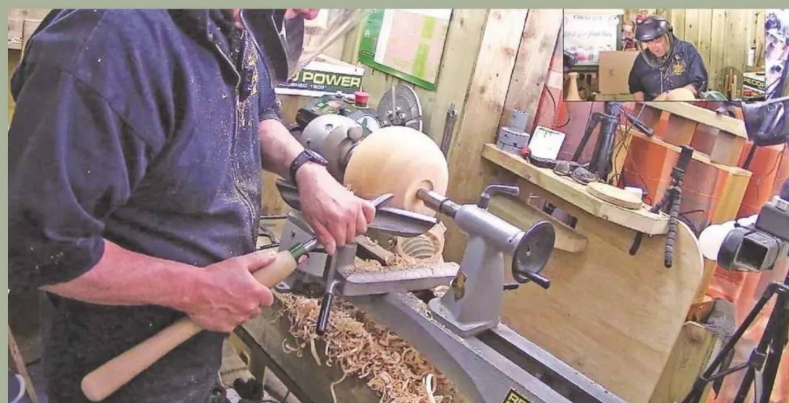
13 As shown in previous photos, leylandii can be very furry, and I find the best way to improve the cut is to employ a shear-scraping method. Here, I use a freshly-sharpened swept-back bowl gouge with my back hand held down at an angle of 60° or more
