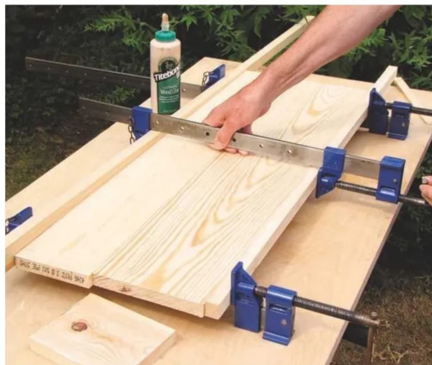
2 If using softwood, you'll probably need to glue boards edge to edge; this will ensure that sufficient width is achieved
