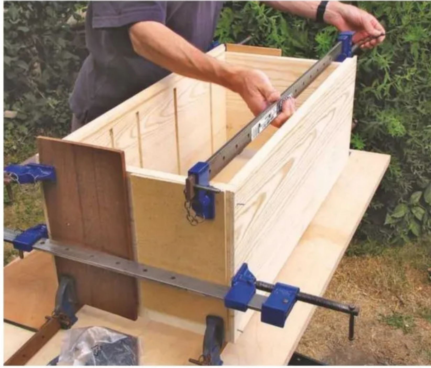
14 Carry out a dry run with sash clamps before gluing the carcass together. If possible, use an exterior glue
