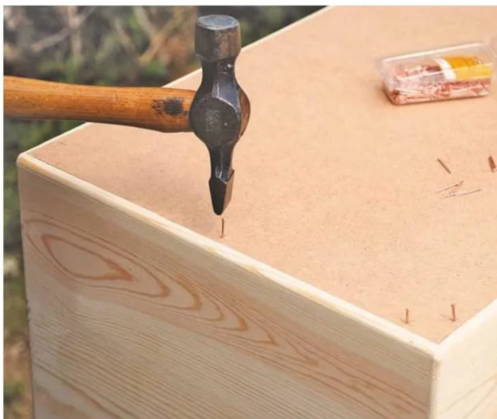
22 The rear panel is made from 6mm MDF. Cut to size and fix to the rebate with hardboard pins
