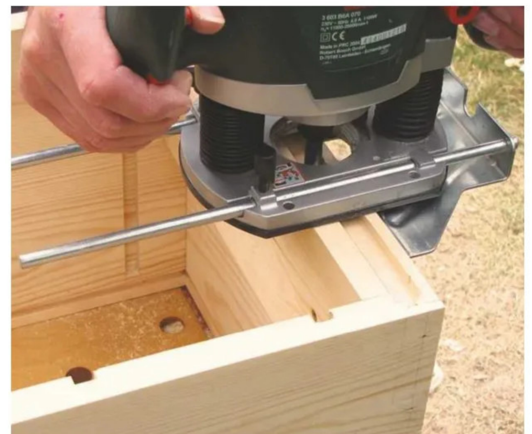
18 For the rear panel, rout a rebate around the inner edges, squaring rounded ends with a chisel
