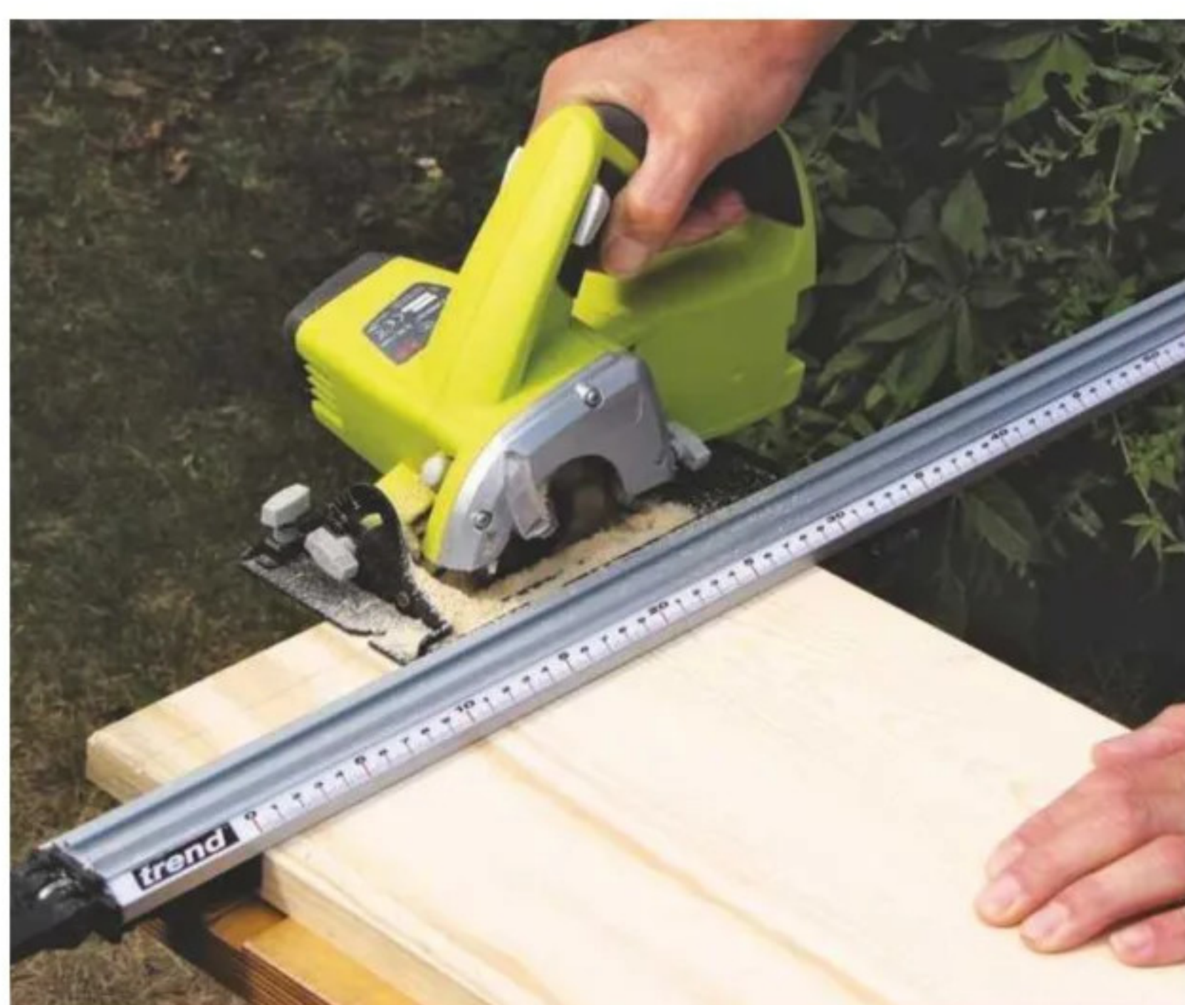
4 Saw the two end sections exactly to length. If using a powered saw, add a guide rail or batten
