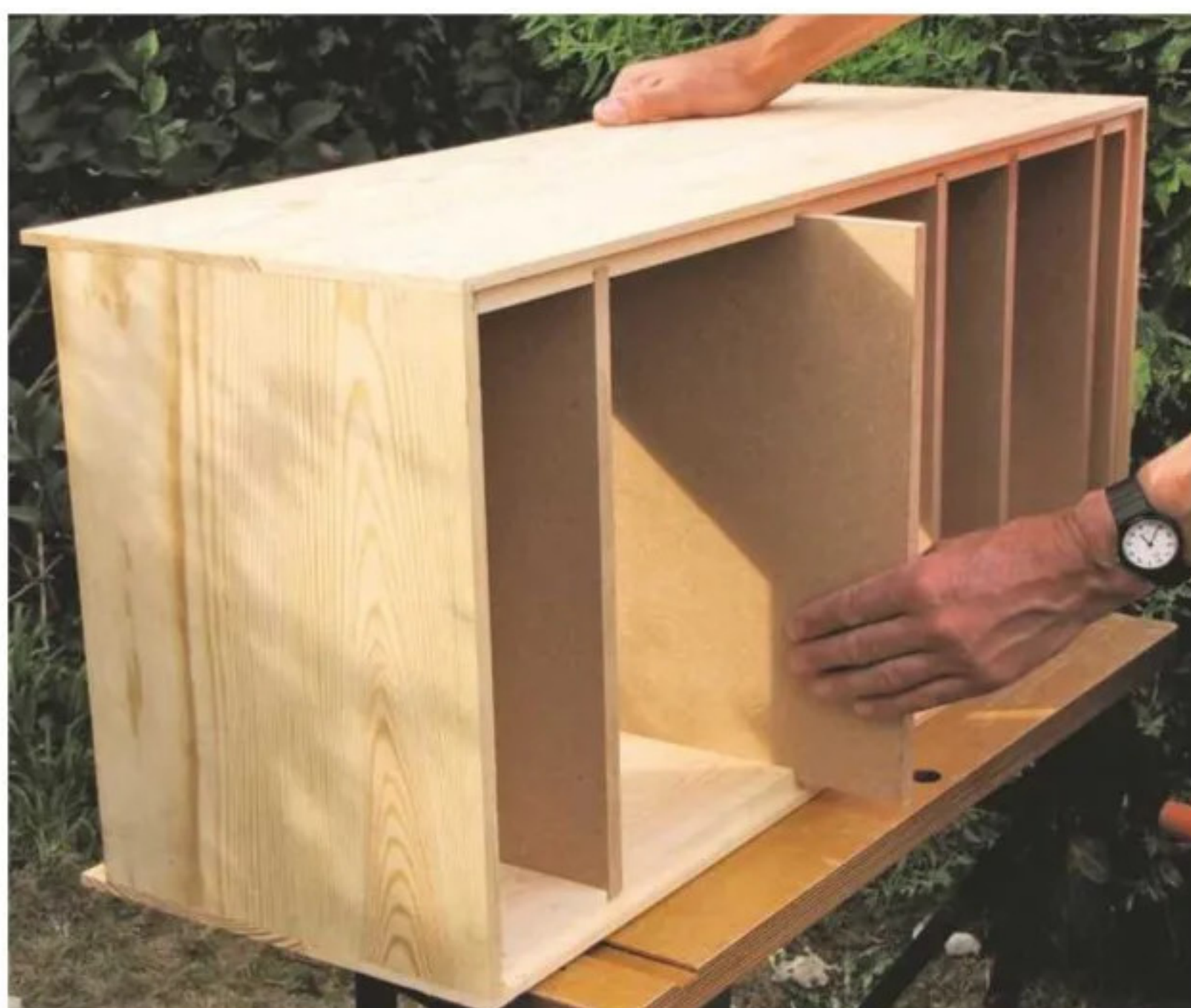
19 Make the vertical dividers using 12mm MDF. Slide these into place without relying on glue
