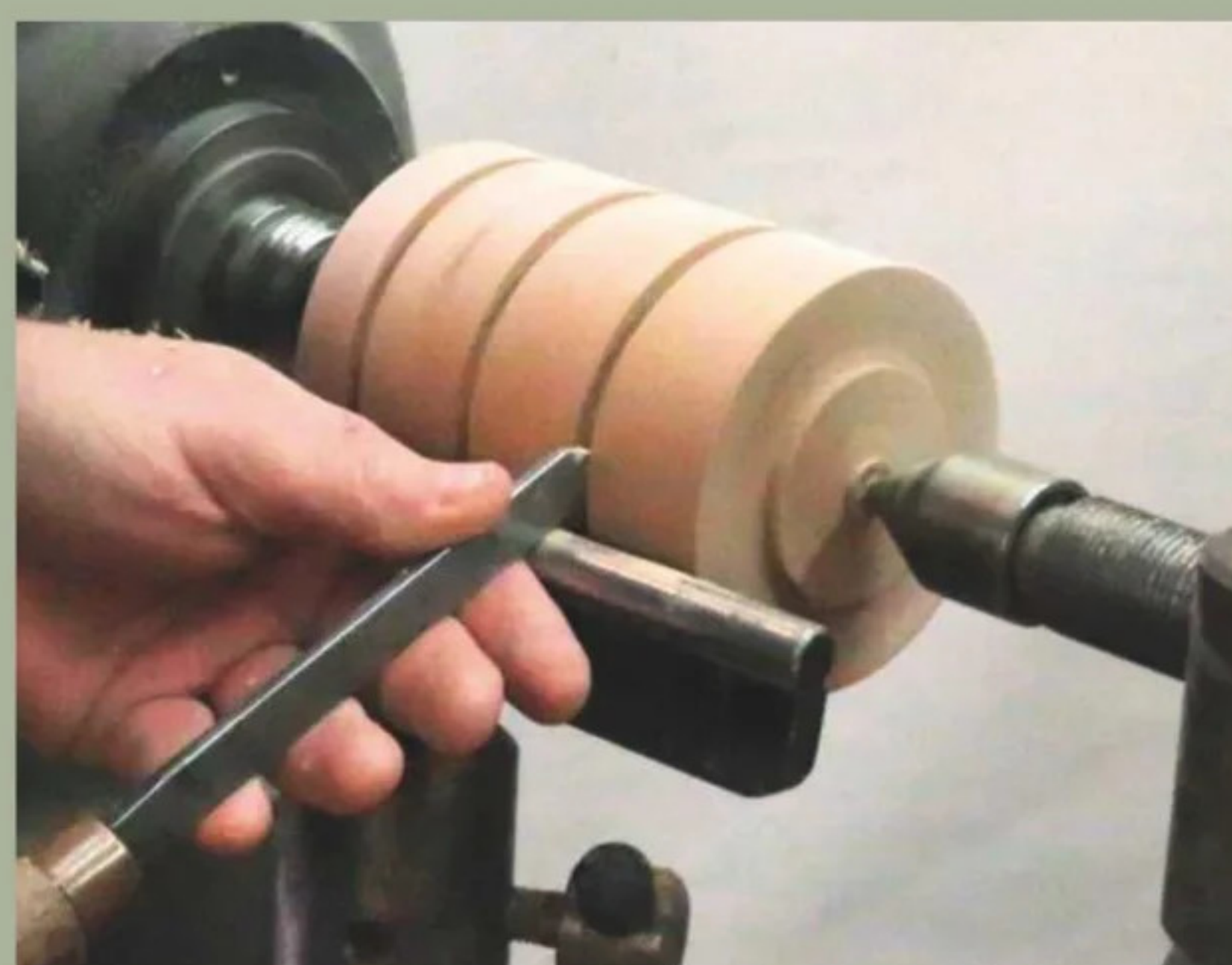
4 ... and make a 10mm deep parting cut at each one of the marks
