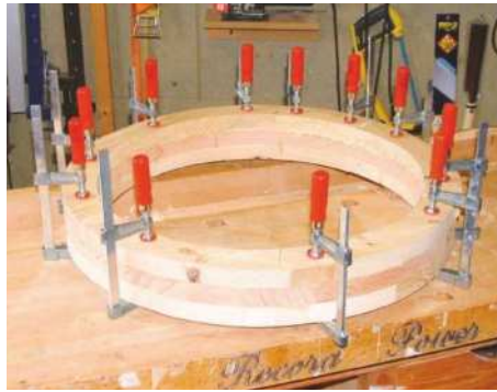
7 Apply glue to all surfaces and cramp the third layer to the frame. Clean up when dry
