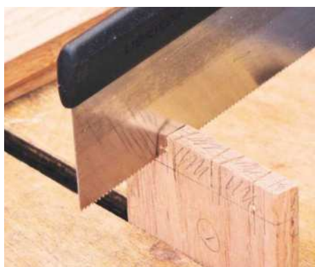
14 Pencil in the waste between pins. Saw down pin sides to form the sockets, ensuring to keep the blade level
