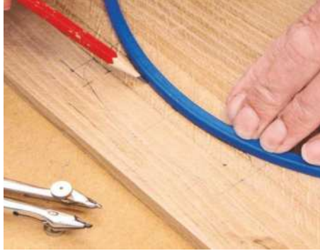
23 Draw the handle cutout with a flexible curve or arched steel rule. Ensure to allow sufficient width for a sanding drum
