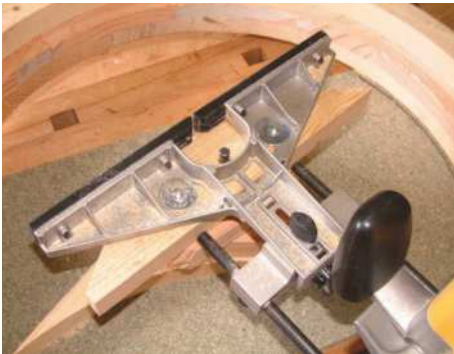
9 Screw a piece of wood to the router fence and drill an 8mm hole – the trammel centre
