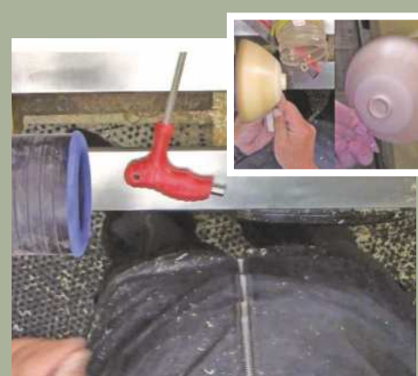
26 I used my 100mm vacuum chuck to hold the small bowl while the foot was being turned, following the same method as before...
