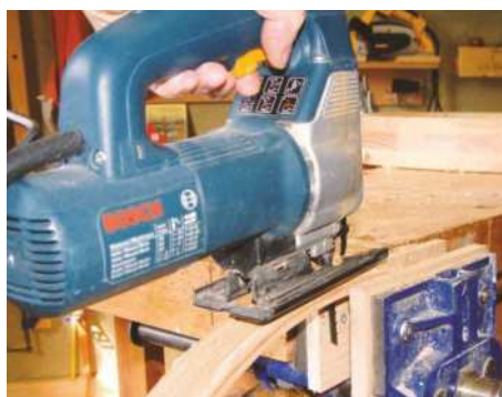
13 Cut the beading to width with a jigsaw, cleaning up the surfaces with a block plane
