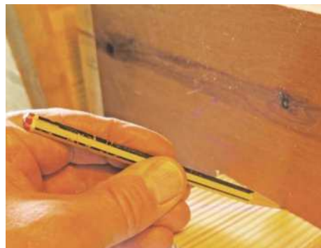
11 Marking a stretcher for the through mortise
