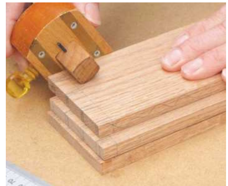
9 Set the gauge to 5mm and mark the rebate for the bottom slats. Pencil in waste to be removed between the tails
