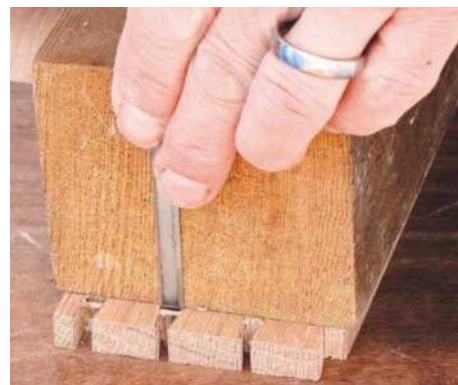
12 Next, cramp the square timber block along the shoulder line; this will keep the chisel upright when it comes to paring back between tails
