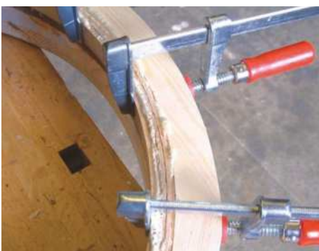
12 Glazing strips are laminated from 2mm thick oak strips, which are glued together inside the frame
