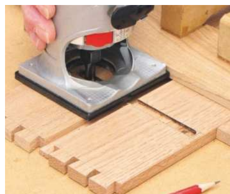
18 Cramp parts together and cut 3mm-deep housings for the dividers. Run the router against a guide batten
