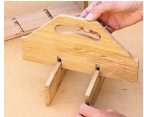
27 Slot the handle and dividers together. Mark out halving joints and carefully cut away the waste
