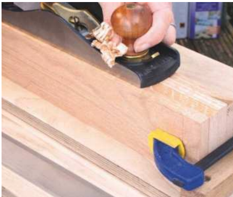
4 Trim ends square on a shooting board. Cramp pieces together, face edge down, and plane to width
