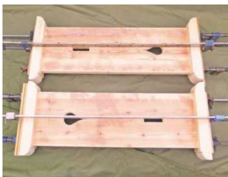
15 Gluing and clamping the table ends
