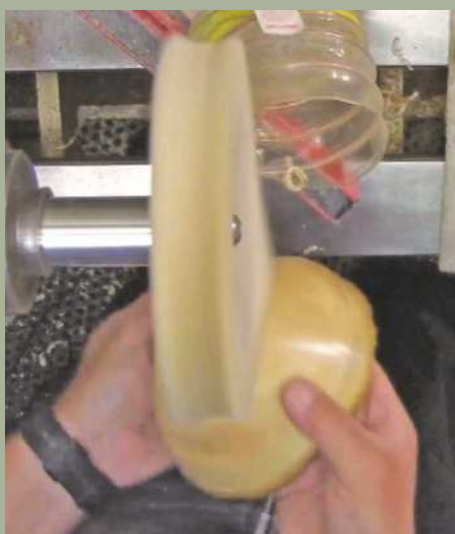
27 ... then sanded and finished with carnauba wax followed by the buffing system
