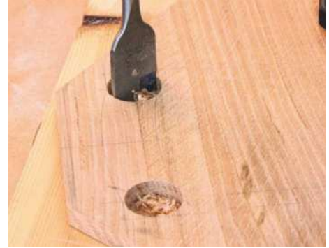
24 Mark hole centres and cramp the board to the backing material. Bore the cutout's ends with a 25mm flat bit
