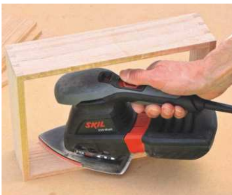
29 Rout a small decorative chamfer along the edges of the tray and dividers, then sand with a 180 grit abrasive disc
