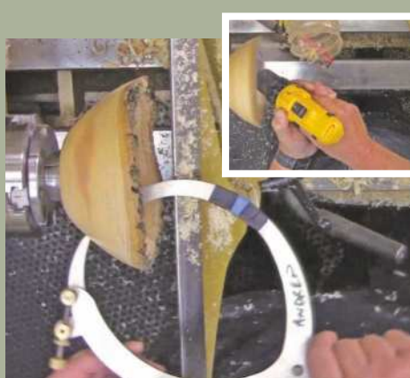
25 ... checking the wall thickness with scissor callipers. Once I'd finished turning the bowl and having achieved an even wall thickness, I sanded using the cordless drill mounted with various arbors
