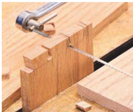
11 Remove waste between the tails with a coping saw, keeping blade teeth clear of the shoulder line
