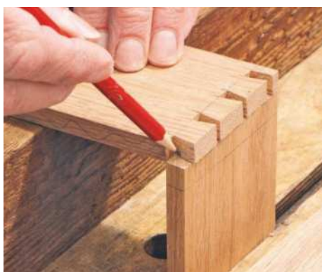
13 Cramp the pin board in a vice and lay the tail piece across horizontally. Carefully mark out pins from the cut tails
