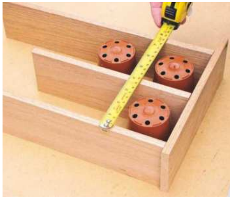
5 Mark each tray component for width and cramp together. Place on a flat surface and plane to width
