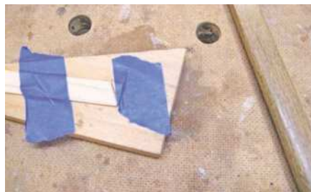
A piece of masking tape acts as a third hand or clamp to steady the strip
