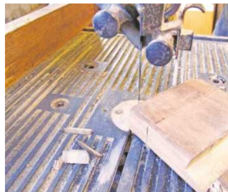
5 Once the trench has been cut, the hard work is over. It takes only a few seconds to trim the corners on a bandsaw...
