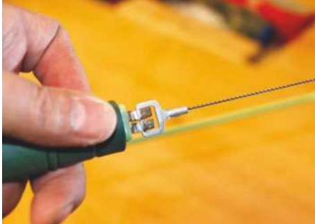
The spiral blades fit to heavy square holders with solid alloy loops
