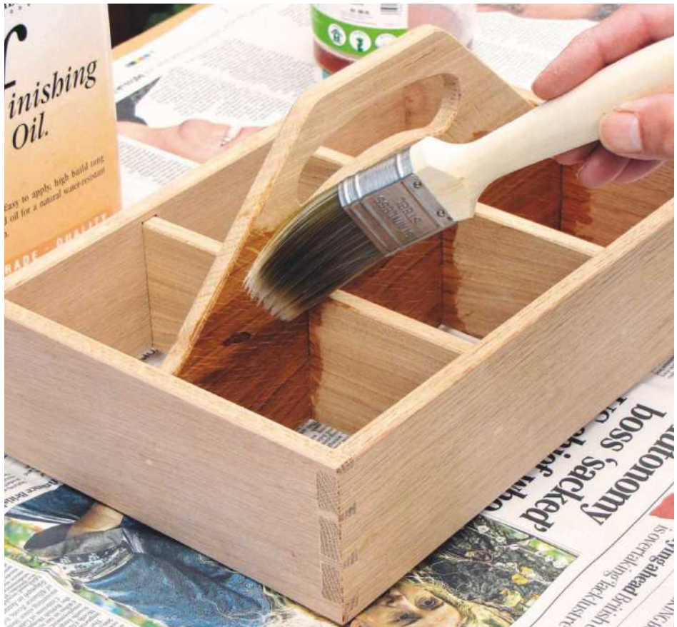
30 Brush on two coats of finishing oil, wiping off after a few minutes. Alternatively, add wax if the project is intended for indoor use
