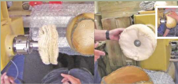
20 Using both the Chestnut and Beall buffing mops, I applied a coat of Carnauba wax with them running at 1,400rpm. It's important to protect the turning using large bubble wrap or a towel, for example, in case it strikes the lathe bed. If you're not careful, the mops can sometimes grab the piece from your hand. To eliminate this, I hold the piece in the 8 o'clock position, taking care to ensure I don't catch the natural-edge
