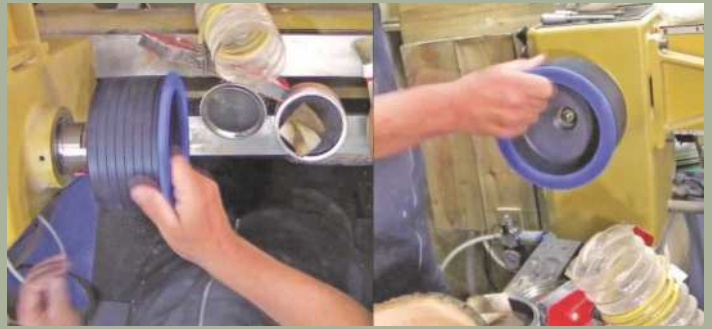
17 In the photos here, I'm holding the bowl in my vacuum chuck at 150mm diameter. If you don't have one of these, you can always make a dome chuck with anti-slip mat supporting the bowl, using tailstock pressure, and sand the last part. You can also remove the button in the foot's centre or make a jam chuck if the edge is flush instead of natural-edged
