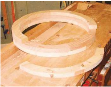
6 Cut and mitre oversized segments for the final layer, using the frame as a base
