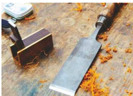
The plane features an upright 90° positioned blade setup for uneven hardwoods
