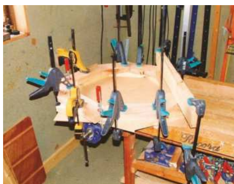
4 Repeat with a second layer, ensuring vertical joints are staggered, then glue up
