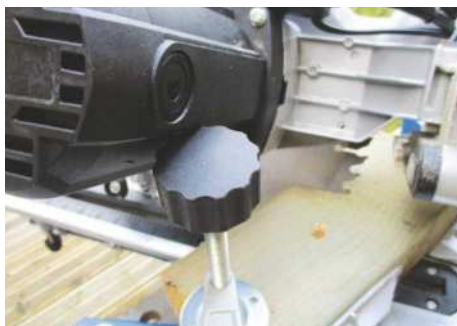
The clamp can sometimes cause an obstruction
