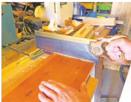
7 Cutting tenons for the table supports
