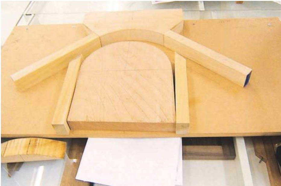
10 To curve the veneers for the back/seat support, I made a dedicated jig. For strength purposes, I used double-thickness MDF but it still needs to be stronger
