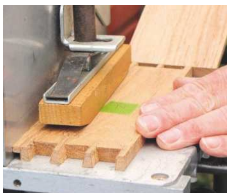
17 Create a 5mm-deep rebate along the bottom edges for the slats. Cut this on a router table to ensure accuracy
