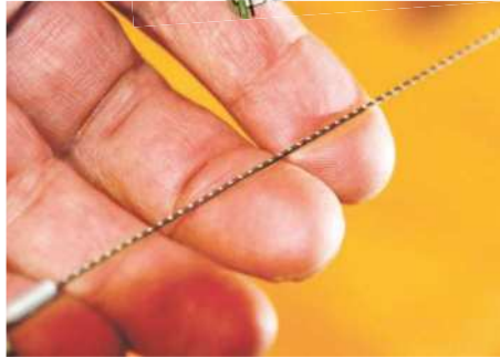
As they're so fine, the spiral blades don't cut as quickly as standard versions
