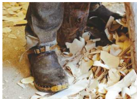
To make a pair of clogs, Jeremy hand cuts the leather uppers and hand carves the soles
