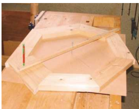
3 Glue the segments together. When dry, clean up the surface and redraw both circles
