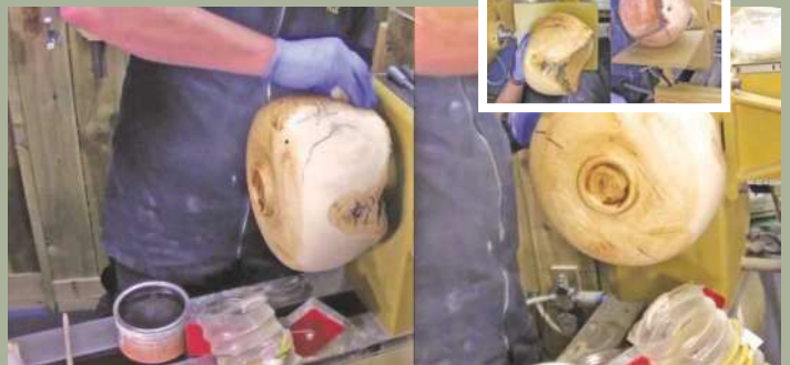
19 This product is applied to the exterior with the bowl held stationary on the vacuum chuck, and for the interior, applied with the bowl sitting on the lathe bed. Again, if you don't have a vacuum chuck, simply apply it both inside and out of the chuck
