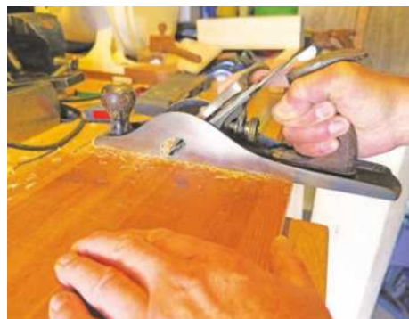
8 Trimming tenons with a bench rebate plane
