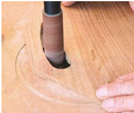
26 Clean up the cutout with a 25mm sanding drum, or rasp and file if preferred. Smooth edges with various grits of abrasive
