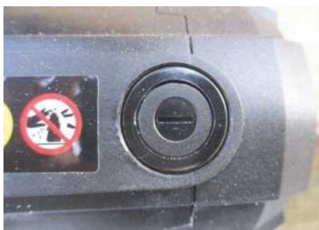
Check the brushes when you find performance starts to dip
