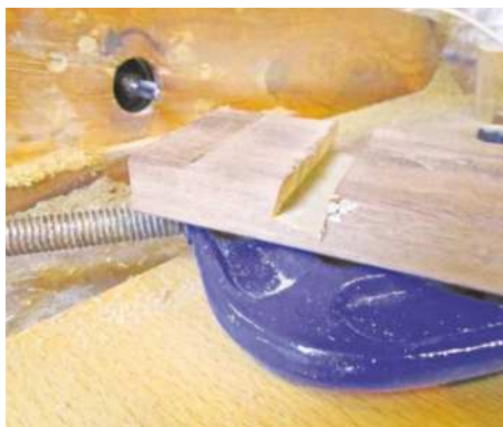
4 There's some minor tear-out on the finished trench, but nothing that can't be removed with a little sanding
