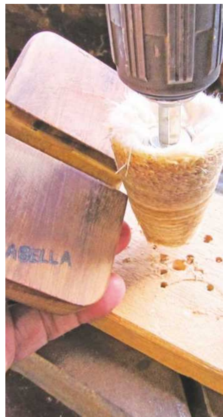
10 The piece was finished by rubbing on a coat of beeswax, leaving it to dry for a few minutes, then buffing on a drill-mounted mop
