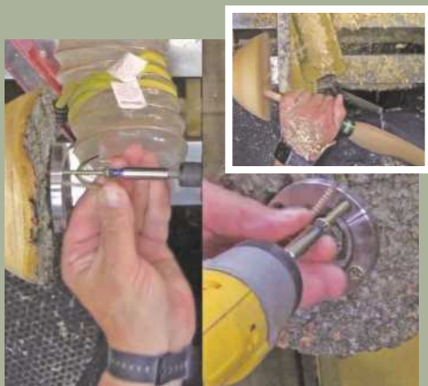
24 I could now remove the faceplate and focus on turning the bowl centre. I made a series of 'V' cuts and removed this central part...
