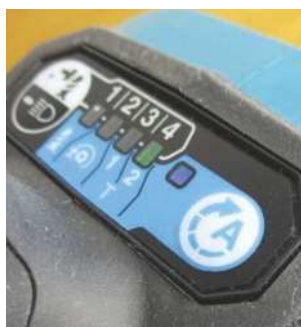
A blue LED indicates that Assist mode has been selected
