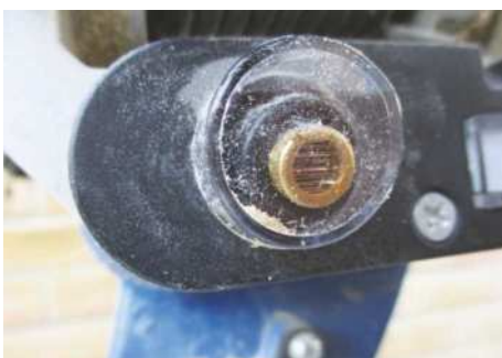
The laser panel requires a dust seal
