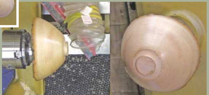
23 Before I reversed the little bowl to remove the centre, I sanded and waxed the exterior, leaving the tenon clean
