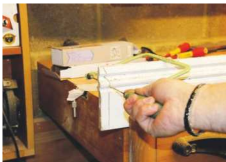
With a standard blade fitted, the frame will foul on some scribing cuts
