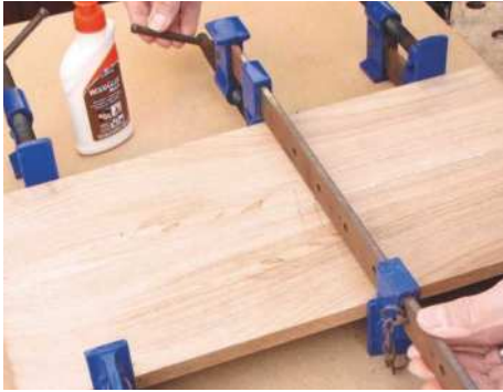
22 If required, glue the boards together to achieve sufficient width for the carrying handle. Thickness when dry
