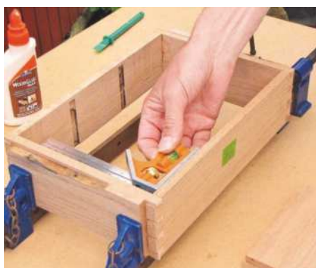
20 Clean up the inner surfaces and check for fit. Glue and cramp up the tray, checking for square
