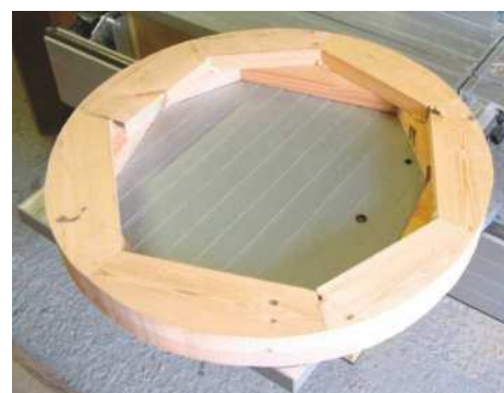
5 Use a jigsaw to cut around the outside, leaving some waste. Repeat for the inner circle
