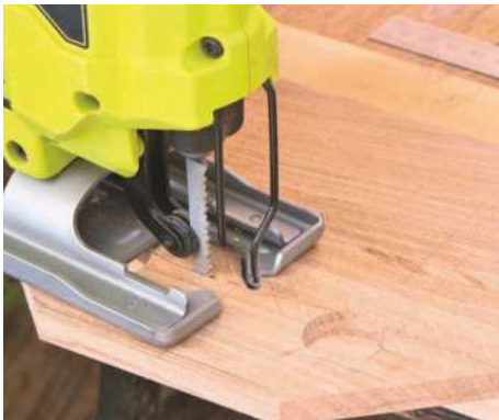
25 Using a jigsaw, remove the remaining waste between holes, then again for sawing the handle's tapered edges
