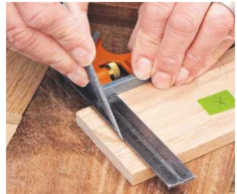
6 Saw sides and ends 2mm over-length for trimming joints later. Scribe shoulder lines for dovetails with a marking knife
