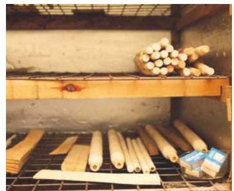
Steam-bent legs and spindles in the drying cabinet
