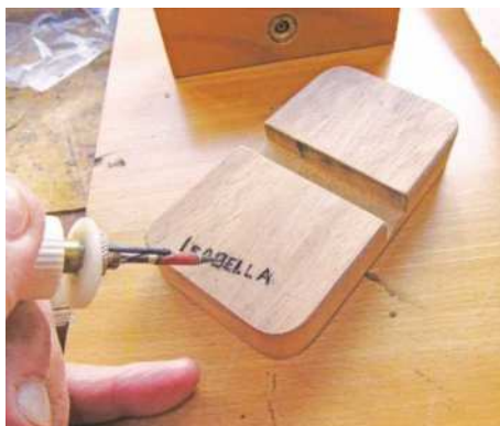
9 To ensure correct positioning and spacing, I find it helpful to draw letters in pencil first before burning them in permanently with a pyrography pen
