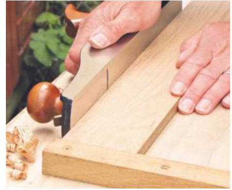
3 True up face edge of sides and ends with a bench plane and shooting board. Check with a straightedge
