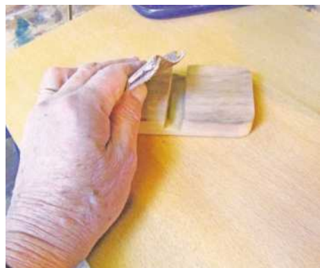
8 A little hand-sanding took off all the sharp edges and slightly rounded the trench's lips, which eliminated the risk of scratching a phone screen
