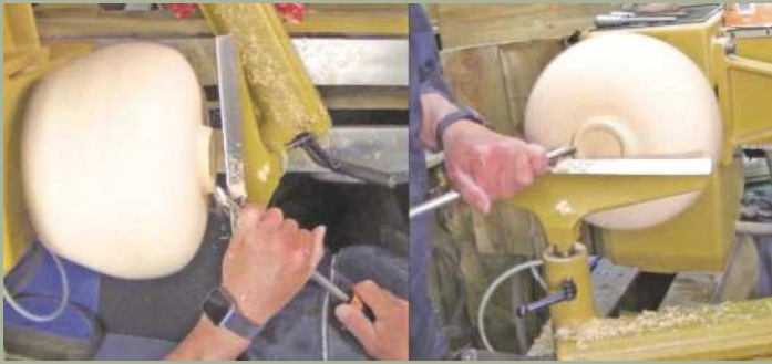
16 Using the 10mm bowl gouge with swept-back grind, I finished turning the foot, ensuring it was slightly undercut so that it'd sit correctly on a surface
