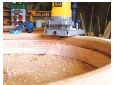
14 Check the fit of the beading in the frame, then add a profile with a rounding over bit
