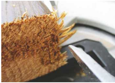
The 24-tooth blade produces a rough finish
