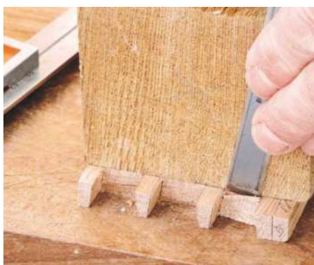
16 Holding the chisel at the correct angle, trim sides of pins – sockets – as necessary. Check joints fit, and adjust as necessary
