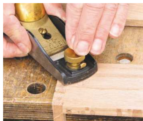
21 Once the glue has dried, trim protruding dovetails flush with a finely-set block plane
