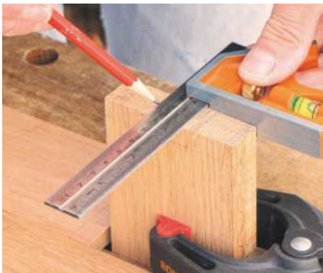
7 Space dovetails to allow for a 5mm rebate at the lower edge. Cramp boards together and square lines across
