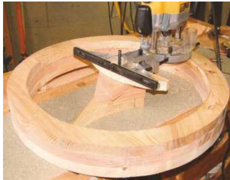
10 Using a long straight router bit, gradually trim both the inner and outer circumferences
