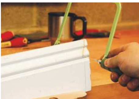
The spiral blade can be pulled, pushed or twisted in the cut without jamming
