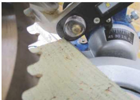
Bevel cutting at 45° reduces possible thickness
