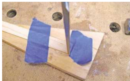
If you need to save the offcut, two pieces of tape can be used
