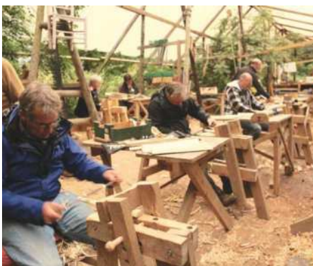
Class at work with the second stage – reducing timber with drawknives while at the shavehorse
