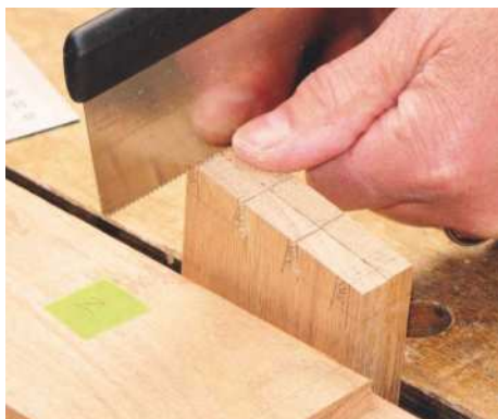
10 Secure both tail boards tightly in a vice, so that they're at an angle. Cut down the sides of tails with a dovetail saw
