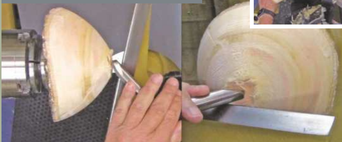
22 Now to turn the core using the same tools as before. To start, I turned the outside of the bowl, removing as little as possible to true it up. I then cut a small spigot to suit the size of jaws I was using
