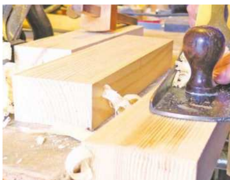
2 Hand planing timber blanks for the feet and top
