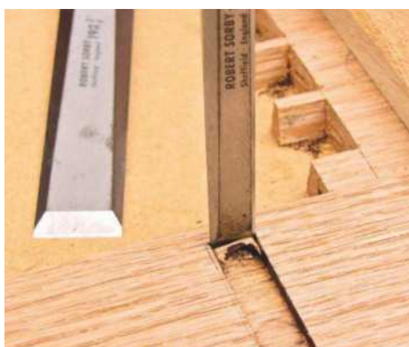
19 Housings are stopped 5mm below the top edges. Square rounded ends neatly with a chisel
