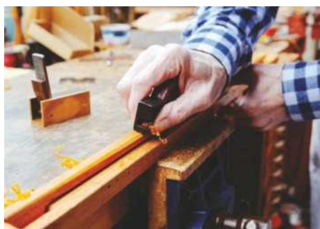
A specialised bow making plane is used to shape the raw material
