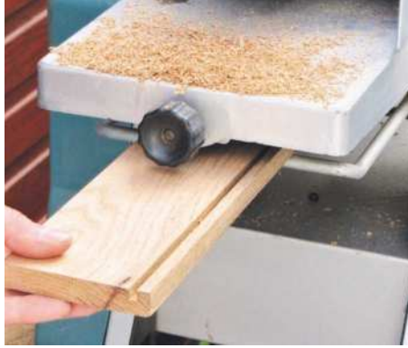
2 Inspect all surfaces closely for defects and cut off damaged ends. Thickness clean timber to 10mm
