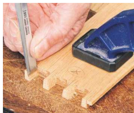
15 Remove waste with a coping saw as before, then pare back to the shoulder line with a bevel-edge chisel
