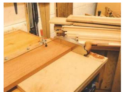
4 With all stock prepared, cut the pieces to length and accurately finish on a shooting board
