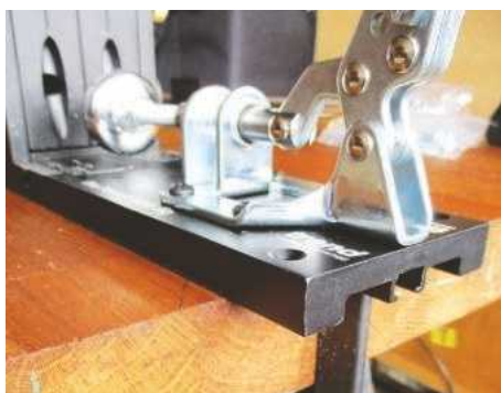
The T-slot can be used for temporary fixing
