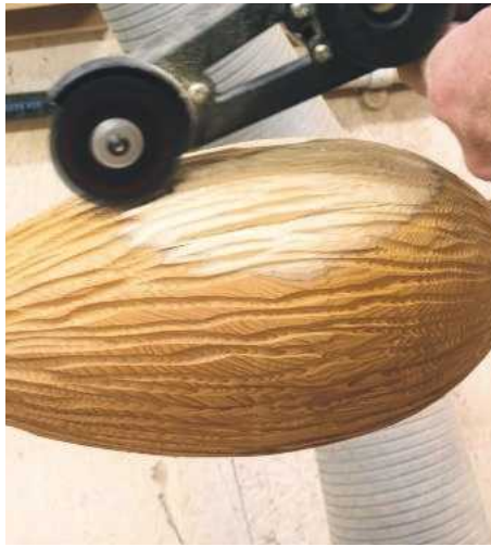
11 I hadn't planned on texturing this piece, but I needed some way of hiding the unsightly split. The Arbortech fitted with mini industrial cutter was used to cut random grooves in the surface, which followed the timber's grain direction
