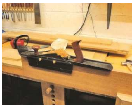
3 After a pass through the planer/thicknesser, edges and faces are finished with a jointer
