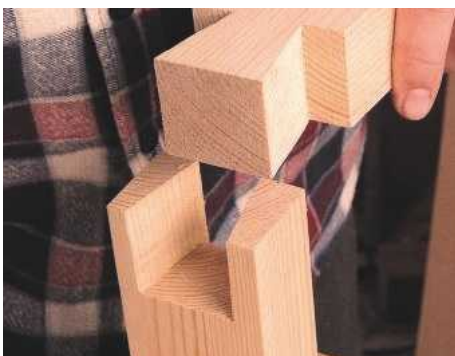
10 The dovetail is aligned with its matching socket before the two slide firmly together
