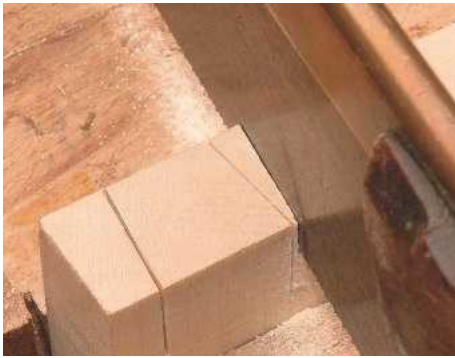
21 Pins are extremely narrow, with the near side little more than a saw-cut width
