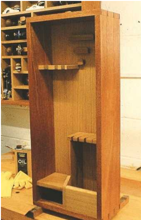
23 ... finish the saw cabinet, which is awaiting French cleats
