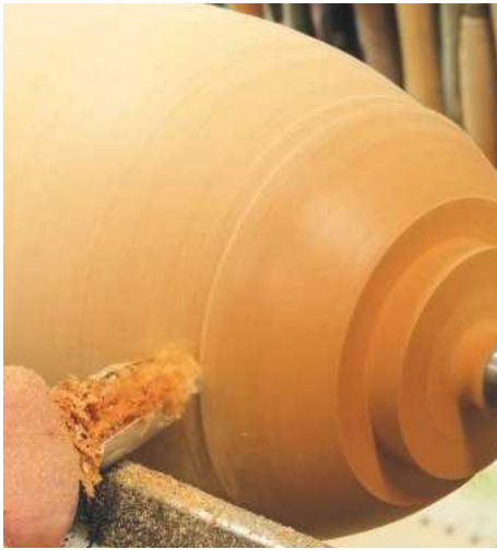
10 Turning an egg shape is completed using the bowl gouge, working downhill throughout the process. Doing so means you're working with the grain and will therefore achieve the best finish off the tool
