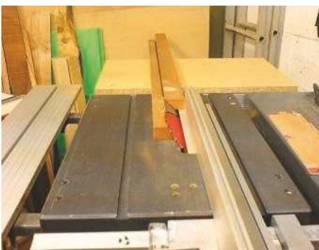
19 Cut the French cleats on a table saw, then clean up before cutting to length
