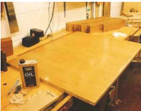
16 Remove the MDF rear panel so you can drill and pre-finish it
