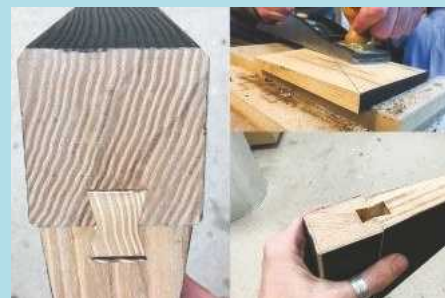
Making of sliding dovetail in rear leg and hand-shaping the drawers
