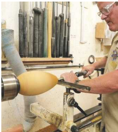
17 Not leaning over the lathe helps to make the whole process much more comfortable and enjoyable. The cutter is angled slightly downwards, which removes some of the force from the cutting edge
