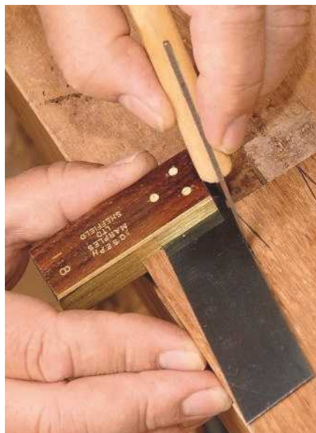
11 Dovetails marked across a board's width are made so fine that the gaps between them won't be any greater than the width of a saw-cut or 'kerf'
