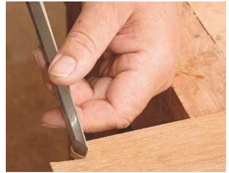
23 The tails' inside corners are pared away to help the joint fit without jamming
