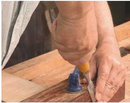
22 Socket bases are pared flat with a wide chisel, using a block to guide the flat chisel back
