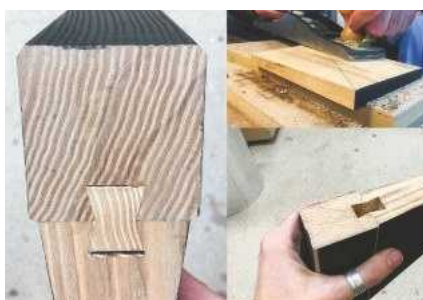
Rear leg sliding dovetail construction and hand-shaping of drawers, as shown on Philip Gay's 'Less is More' cabinet
