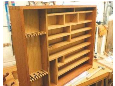
18 The completed plane and chisel cabinet – note cut-outs for storing chisels
