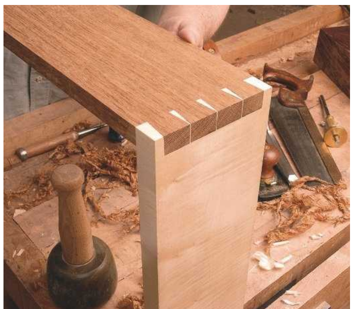
26 The outside of the finished joint shows fine pins emphasised by contrasting wood colours
