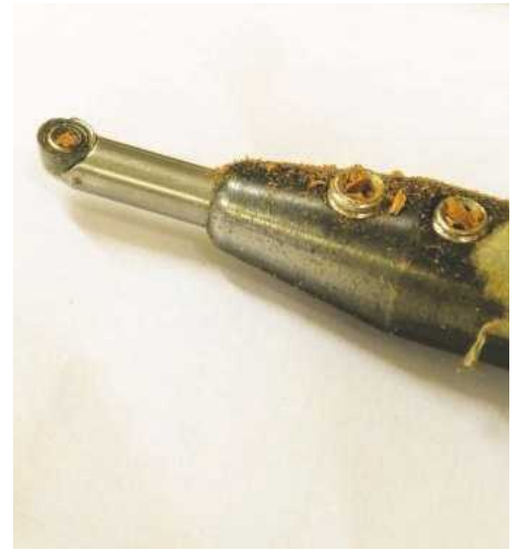
15 This Simon Hope hollowing tool with small carbide cutter is one of the best I've ever used. The combination of a big bar and small cutter is perfect for working blind
