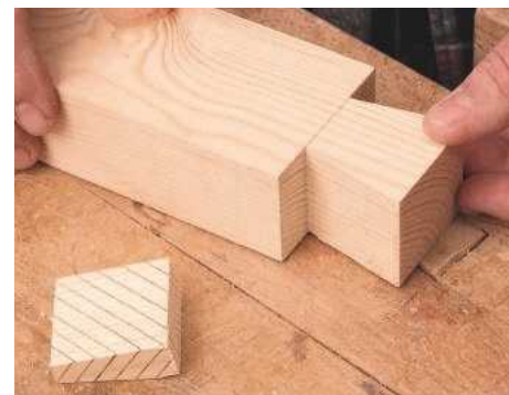
6 With waste cut off each side, the single large dovetail remains
