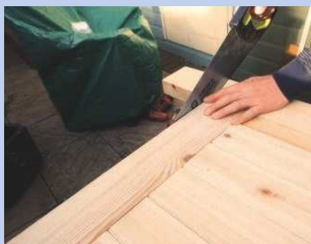
9 Cutting the horns after gluing up
