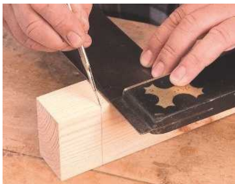
3 The shoulder lines run around the joint. By placing the knife blade in the previous line and sliding the square up against it, all four lines will join up accurately around the wood
