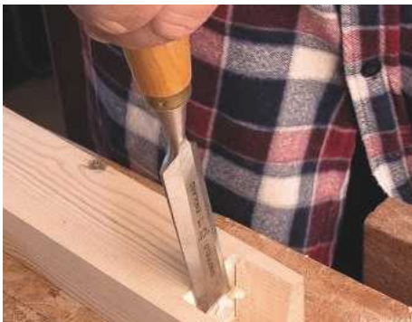
9 Having removed the waste from the socket, its base is pared flat with a wide chisel
