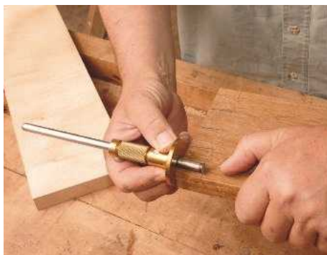
13 Keeping the marking gauge at the same setting, it's used to mark a shoulder line between the tails
