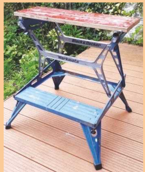
WM625 E05 standing – recognisable owing to its blue steel frame and cast aluminium H-frame Photograph courtesy of Robert Scheepers
