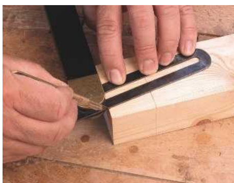
4 Using a bevel gauge to mark both sides of each tail, to ensure they have the same angle
