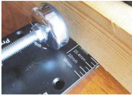
This gauge indicates material thickness...
