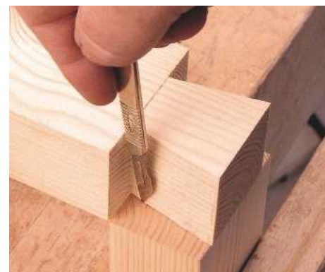
7 The dovetail is used as a template while the socket is marked around it
