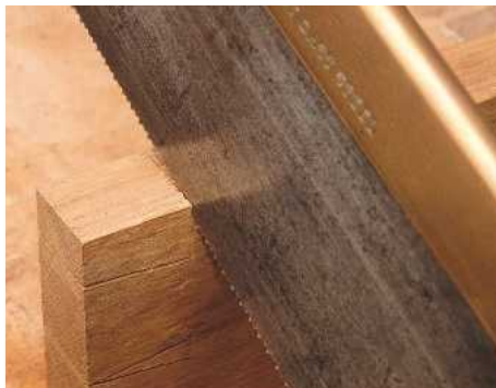
17 Sawing end sockets with the blade cutting just inside the shoulder line's waste side
