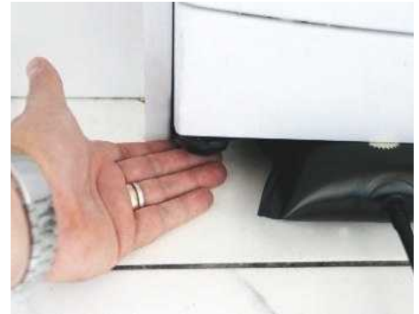
A heavy washing machine, easily supported – an indication of the Easy Air Wedge's lifting power
