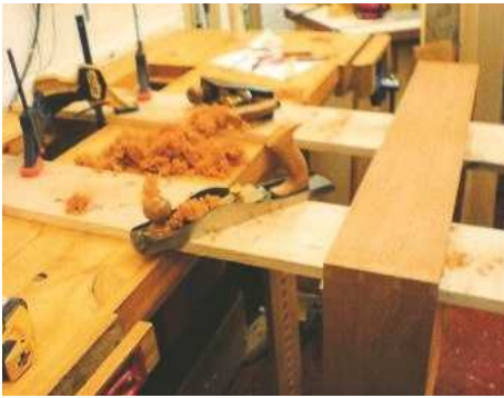
10 Clean out the corners of stopped rebates and pin joints
