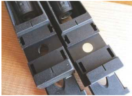
... but has a magnet to hold it to the clamp strip
