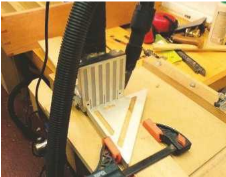
13 When cutting slots in the faces, use a square to register the biscuit jointer...
