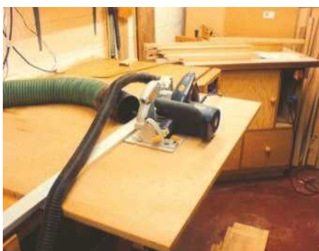
2 The light circular saw, along with clamp guide, is ideal for ripping MDF to size
