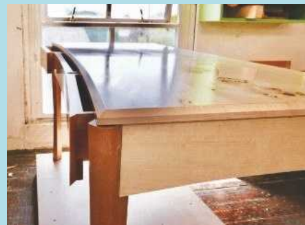
Workshop photo illustrating curve on the front along with drawer angles
