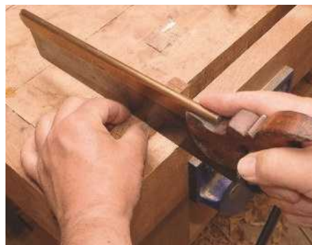
15 The finger and thumb of the other hand are used to guide the blade's position on the knife line
