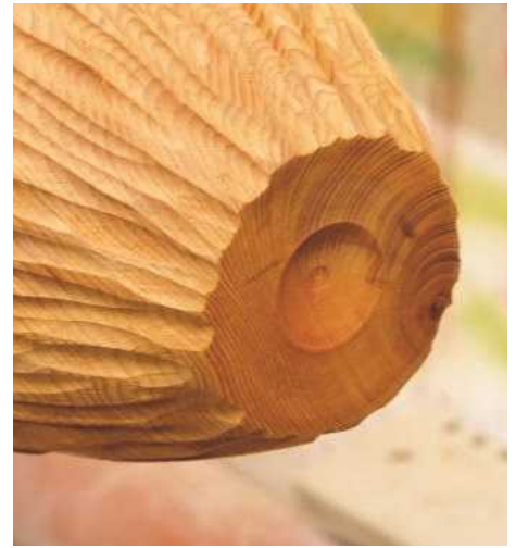
12 When hollowing end-grain, it's advantageous to drill out the centre. I turned a small location hole in the end of the piece using a spindle gouge, which ensures the drill has a perfect start
