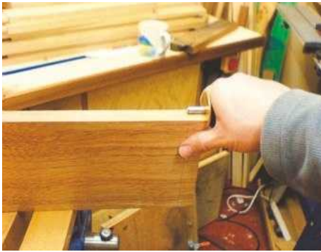
5 Scribe around the boards to mark out baselines for a set of dovetails
