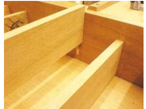
15 Using a biscuit jointer, cut long slots for the dividers and shelves to be slotted into
