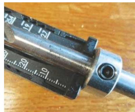
... then lock the depth collar in place
