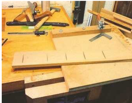
14 ... so that the slots are exactly perpendicular to the sides
