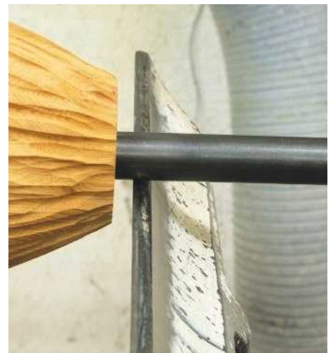
18 Ensure to keep the toolrest close to the work, and wherever possible, try to work over the stem, which is the strongest part. I find it best to keep the tool presented horizontally
