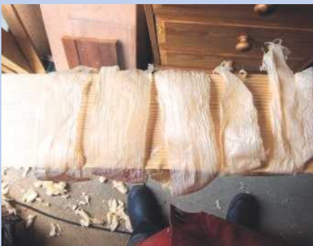
5 Nice wide shavings with a thick Ray Iles plane iron fitted
