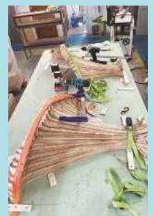
Two halves of the chair being laminated
