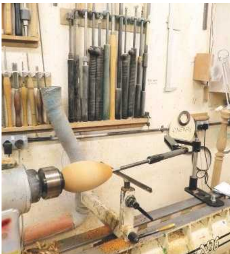
16 The hollowing rig all set up on the lathe. It's important to get a good fixing to the lathe bed, which ensures you avoid any chance of vibration. I carry out initial hollowing without the laser attached
