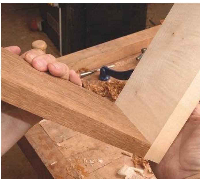
25 As the shoulder lines have been carefully aligned, there's no visible gaps inside the joint
