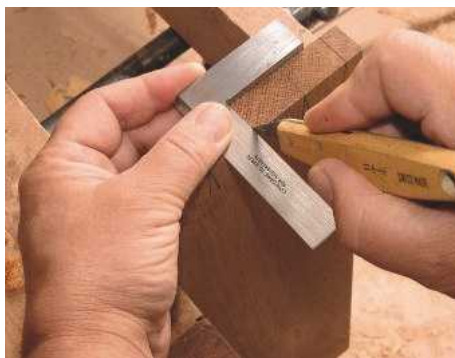
14 The tails' ends are marked across the board at right angles
