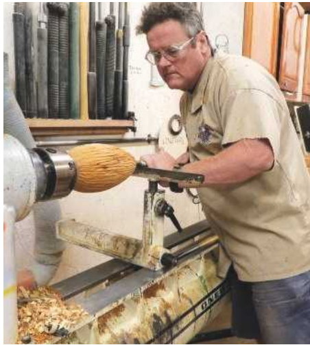
14 This is my usual stance when hollowing on the big lathe. I could transfer the work over to one of my swivel-head lathes, but they're not as powerful as this 3hp Oneway
