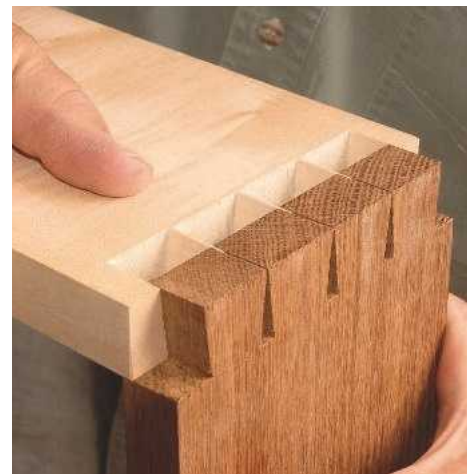
24 The fine dovetail joint is slid together
