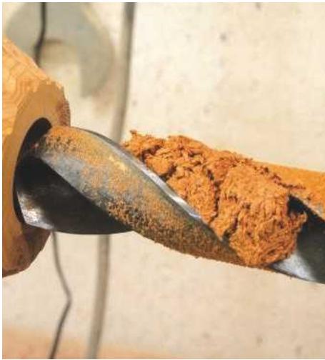
13 I used a twist drill as I like the way the shavings exit through the piece. You can see how these swell once they've been cut. Using a Forstner bit allows the shavings to back up behind it
