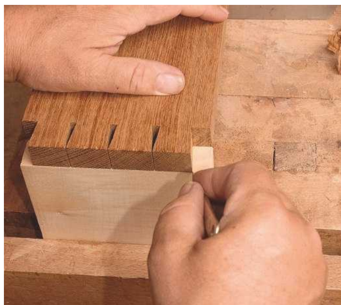
20 The dovetails are used as a template for marking out sockets with a fine knife
