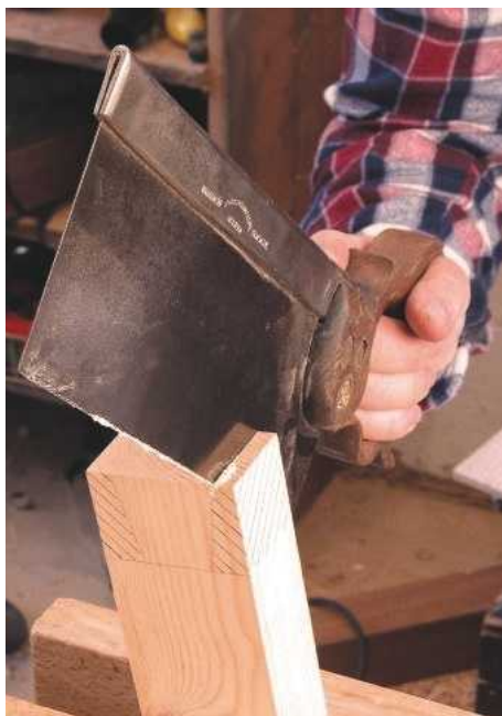
5 Shading pencil lines across the waste area helps keep track of which side of the line to saw against
