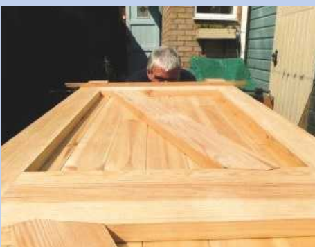
8 Checking for wind before clamping
