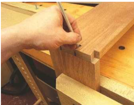
8 ... after which you can use the tail board as a template when marking out the pins...
