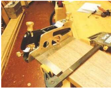
6 Planing a shallow rebate in the pin board makes it easier to align boards later
