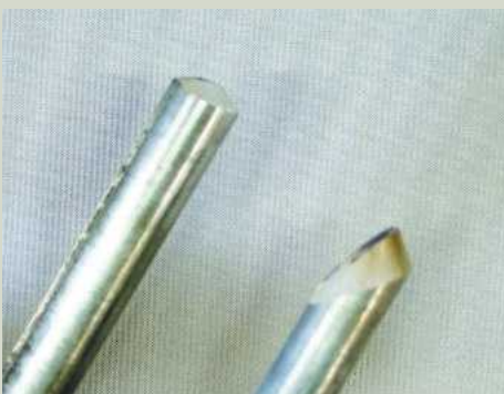
21 A steeper bevel angle helps to overcome this problem...
