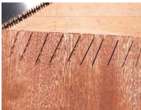
18 ... but acutely-pitched dovetails can involve a lot of work
