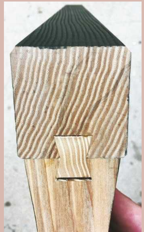
8 A double dovetail joining block was machined up deliberately smaller; this ensured the pieces were pulled together tightly
