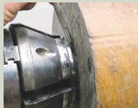
1 Ensure your chosen blank sits firmly against the screw chuck
