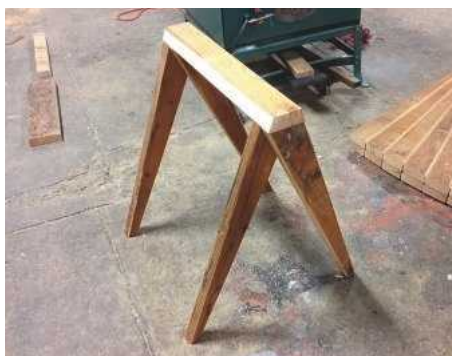
18 The top plate is flush with the A-frames' outside edges
