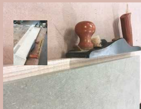
3 Using a plane on its side to shoot veneer, ready for bookmatching. The veneer's joining edge needs to be perfectly straight so that the join is – hopefully – seamless
