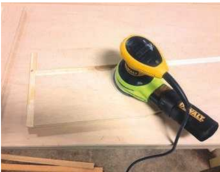
7 Smooth surfaces with a 120 grit abrasive disc mounted in an orbital sander
