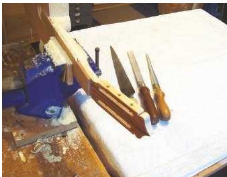
50 Shaping the headstock
