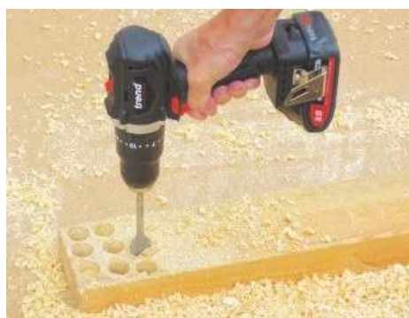
To test drilling performance, I bored a series of holes in 50mm-thick softwood with a 25mm flatbit
