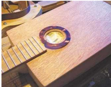
54 Testing the rosette's position
