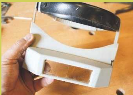
5 For finer teeth, a magnifying visor is well worth the investment
