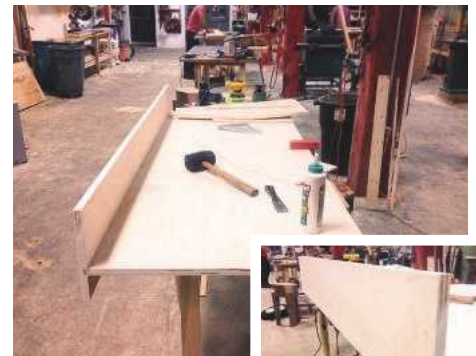
9 Secure the back by pre-drilling and screwing with Spax MDF screws
