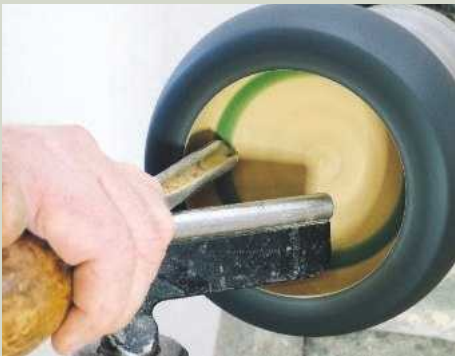
19 Swing the handle through about 100° while cutting the area coloured in green
