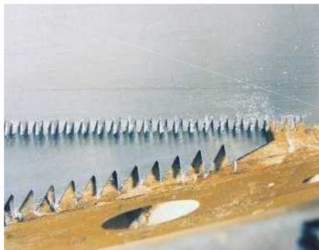
16 The needle-point profiles on Japanese saws are difficult to sharpen
