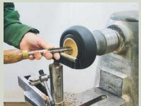
15 Gently swing the hand to this position as you cut down the inside wall
