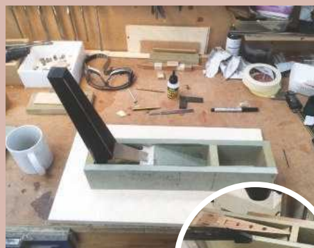
13 The back leg required a jig so it would sit square and flat to the pillar drill. The holes were then drilled and inserts fitted
