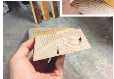
16 The two top plates have a 5° taper on each edge
