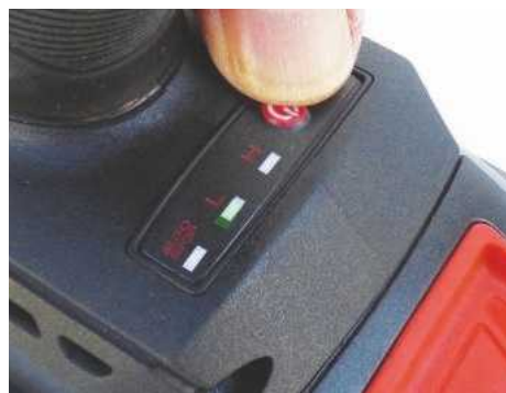
To switch between variable speeds, you press a tiny push button at the handle's base
