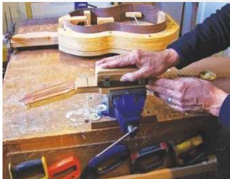
48 Fret edges are filed to 90°
