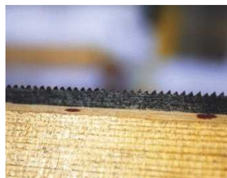
13 For speedy use, I like to file rip saw teeth a few degrees back from 90
