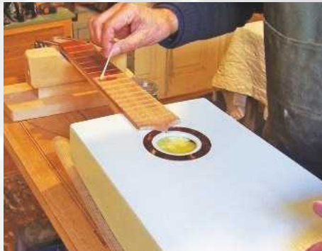
64 Oiling the fingerboard
