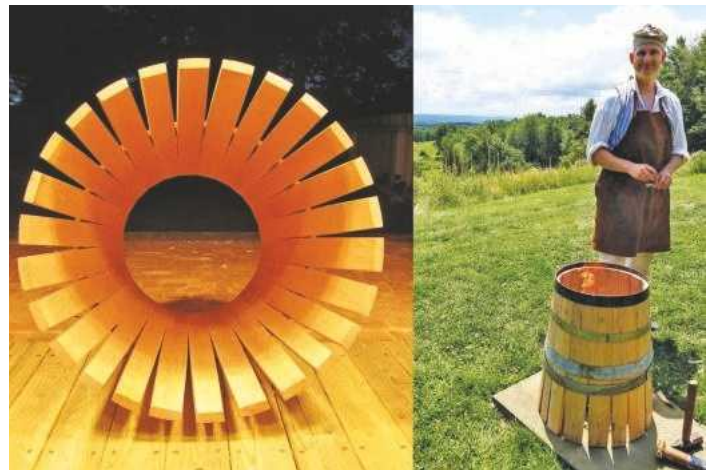
5 Left: A hogshead-sized barrel – 63 gallons – just before trussing – bending of the staves to make a barrel shape; right: Marshall Scheetz, of Jamestown Cooperage, heating the barrel staves to soften the wood so they'll bend when the truss hoops are hammered down onto the cask's splayed end. The fire is contained inside a small metal basket called a cresset
