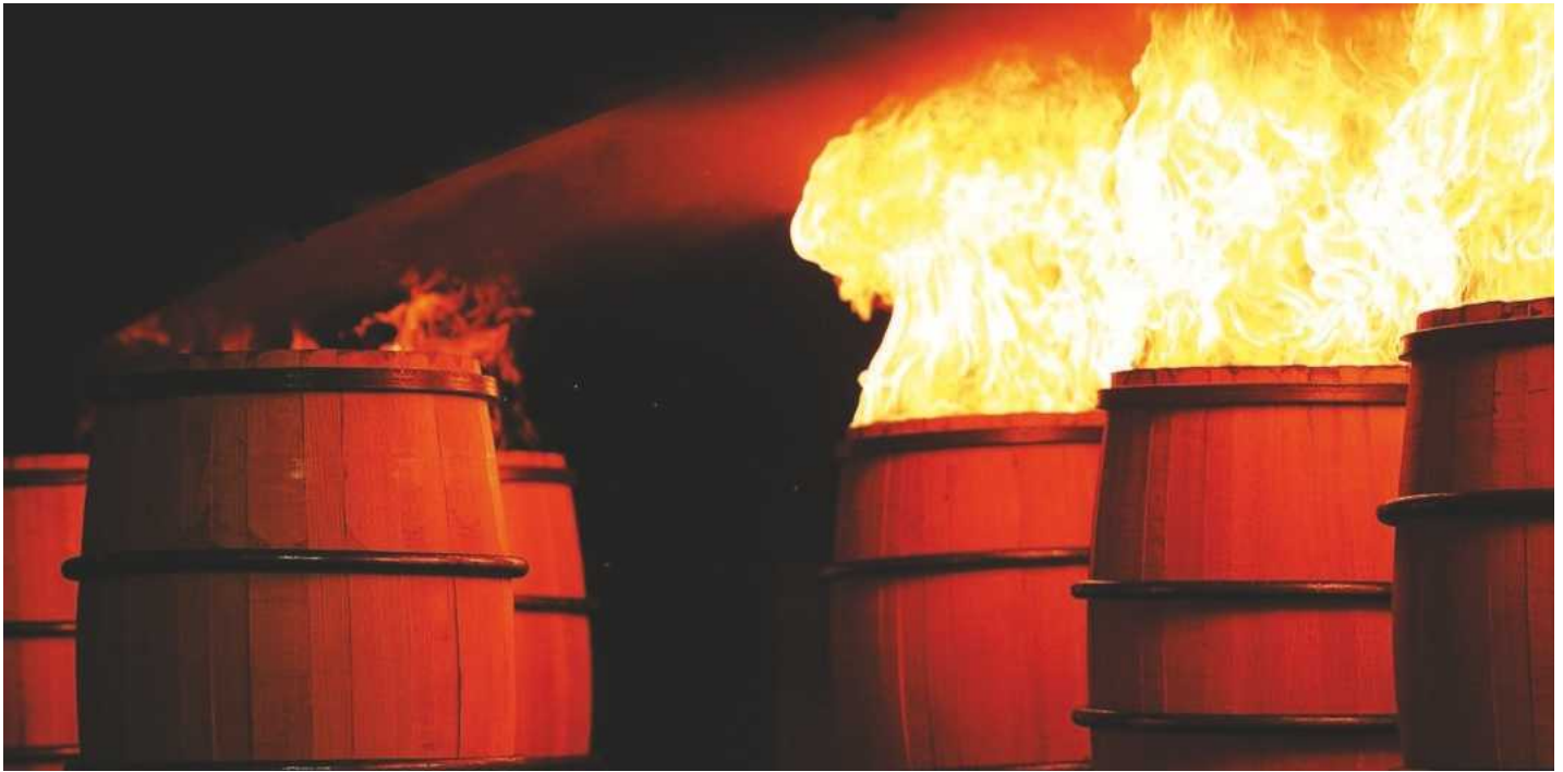
6 The degree to which a new barrel is toasted and/or charred can have a huge effect on a whisky's flavour. Brown-Forman Cooperage makes hundreds of thousands of barrels a year. Photograph courtesy of Whisky Advocate
