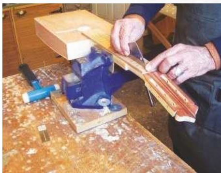
49 Testing the frets for level
