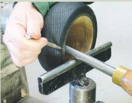
20 A common problem with undercut vessels: the rim interferes with the tool shaft
