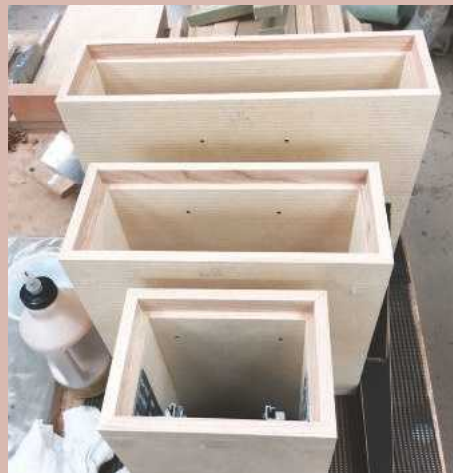
10 Each piece required rebates on the front and back, as the drawer fronts are inset in addition to the back panels. When viewed with drawers closed, this creates a slimmer look to the box carcasses
