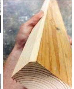
15 Running a chamfer bit across the edges adds a nice finish
