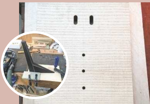
12 All fixings for the back leg needed to be sorted prior to glue up. A combination of dominos and mechanical fixings were used; this ensured a good solid glue joint, which could be clamped up using bolts into threaded inserts
