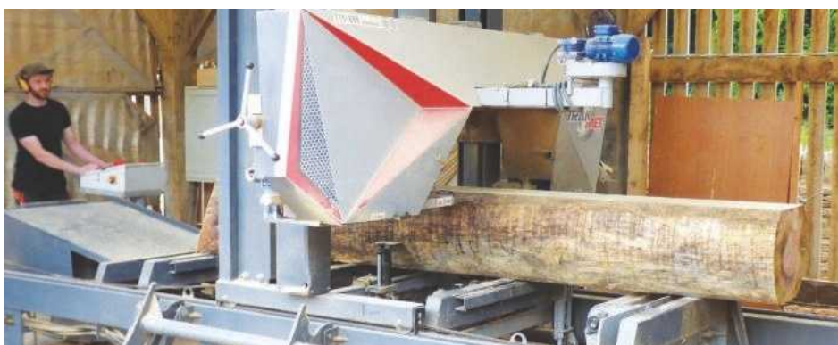
8 Josh Hayden was giving regular demos of the newly installed Trak-Met horizontal bandsaw mill
