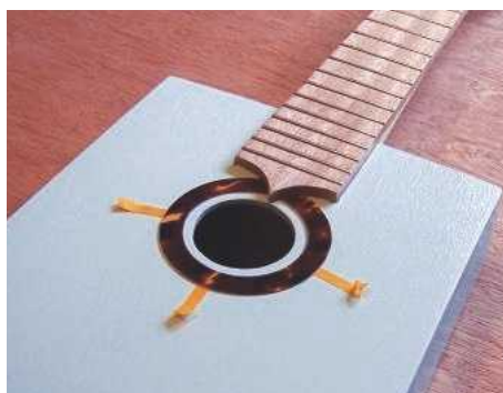
58 The rosette in position
