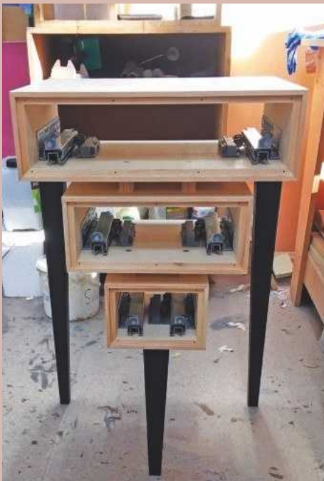
24 Fitting back panels and runners
