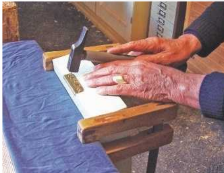
63 Tapping the hitch pins in at an angle
