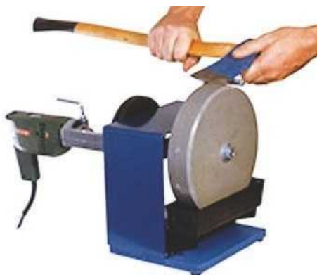
1972: An ordinary portable power drill was used to turn the grindstone; this model rapidly became popular
