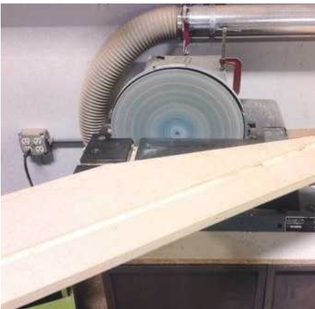
6 Before assembly, sand all the edges. I used a disc sander but a true edge sander is preferable, owing to the long lengths
