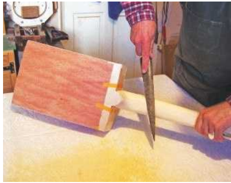
51 A final profile is given to the neck and heel
