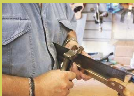
1 If the saw requires little work, I set first, but if bad, it may need heavy topping and dressing beforehand
