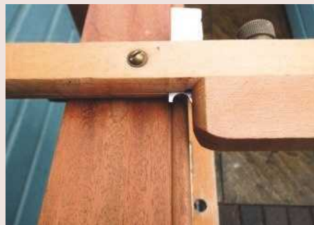
Bolection profile in a homemade scratchstock, which makes use of a tenon saw blade
