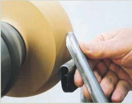
9 Take fine finishing cuts to clean up the surface
