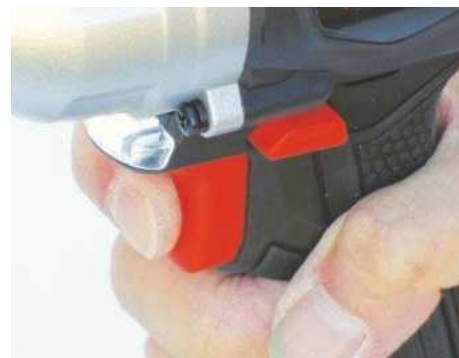
The T18S/ID has a standard trigger and forward/reverse selector above
