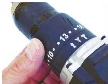
Two collars in front of the gearbox allow you to select torque or tool function
