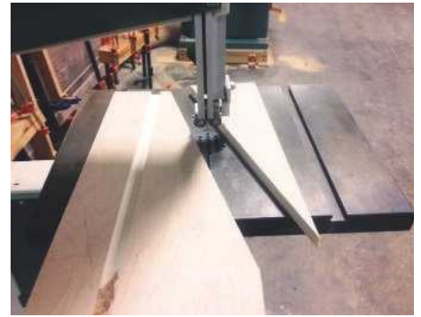
5 Cutting the taper on a bandsaw. Shown at the top of the photo is the 146mm mark and at the bottom right-hand side, the point that's 254mm from the back of the piece
