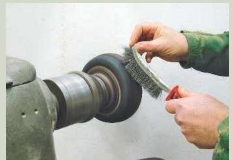
12 ... then brush off the resulting carbon with a stiff wire brush
