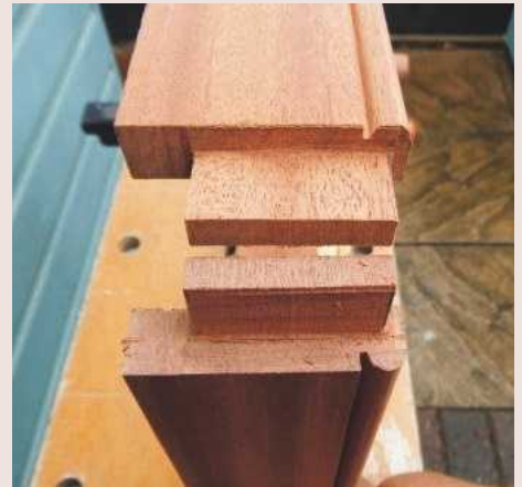
Shallow tenons connect the legs
