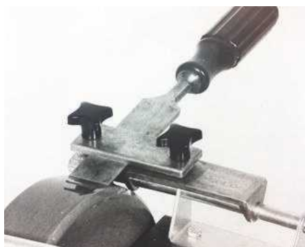
1978: The first generation Tormek Square Edge Jig. At this time, the Tormek Universal Support was yet to be invented
