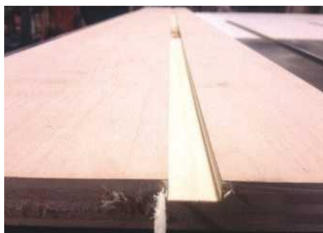
2 Here's the finished back piece. The dado starts 100mm up from the bottom – left – and is 20mm and, a little under, 10mm deep
