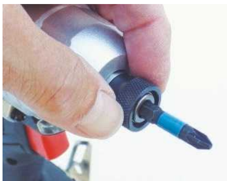
To insert or remove a bit, you simply pull the spring-loaded, knurled steel collar forward
