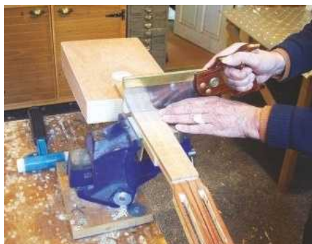
44 Fret slots are cut to the correct depth
