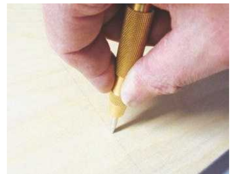
The automatic centre punch is a time-saver
