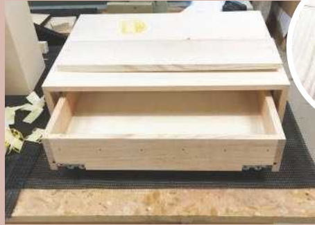
19 Fitting the drawer fronts with spacers, prior to scorching and ebonising
