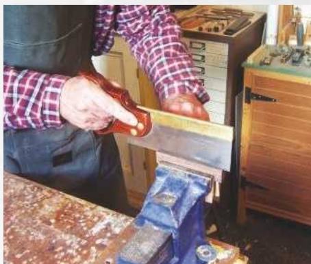
66 A fret slot is required along the top of the bridge
