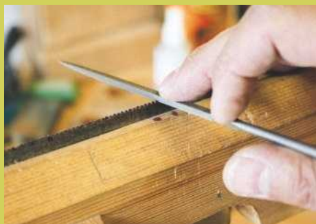
4 The file must be at least twice the depth of the gullet, but not so big that it deforms the tooth profile
