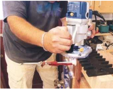
4 Another version of the fixed-comb jig, however, cuts the tails with a dovetail cutter and a straight for the pins...
