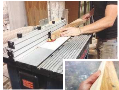
15 Running a chamfer bit across the edges adds a nice finish
