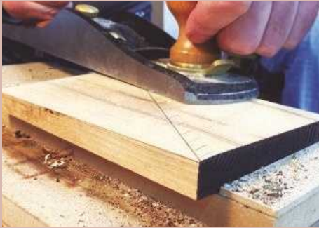
18 Shaping the drawer fronts into tapers for each of the four corners
