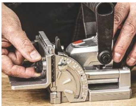
Tilting fence and adjustable cutter height fence setting for traditional jointing styles and bespoke constructions
