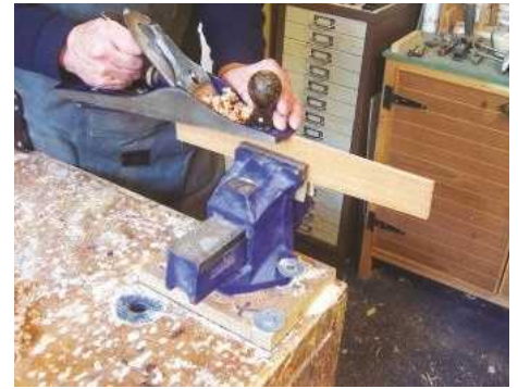
39 Truing the fingerboard edges
