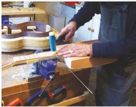
46 Tapping in frets with a dead blow hammer
