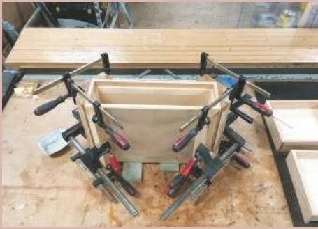
15 The first glue up. To aid this step, custom mitre blocks were built for each of the boxes
