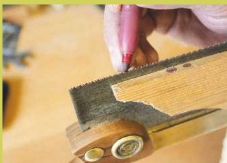
2 Touching in the teeth and gullets with a marker pen makes it easier to see when you start to file
