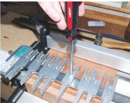
6 The original Leigh jig offers real versatility...
