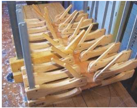
38 Two pieces of padauk are laminated to make a fingerboard
