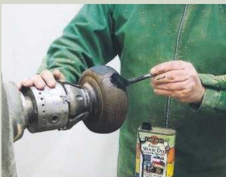
13 Use ebony wood dye to blacken the surface
