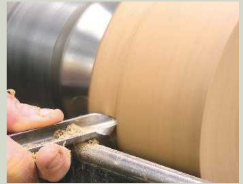
3 ... and a push cut to true up the edge
