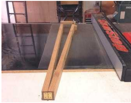
14 One of the legs showing the wing nut and slot at the other end for adjusting the angle; the stop block to set the workpiece against, and a simple taper leg jig, with hinge at one end
