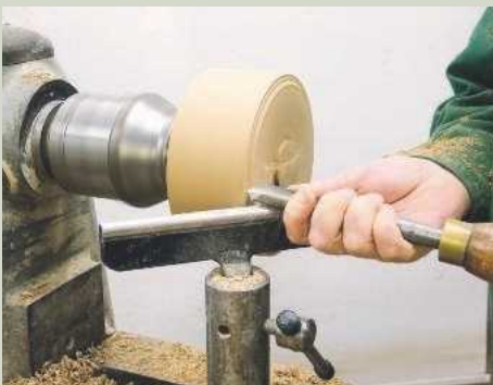
5 Begin shaping from the bottom corner...
