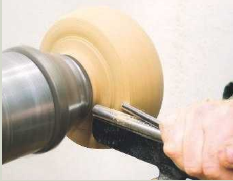
10 Cut the rim using a small gouge held on its side
