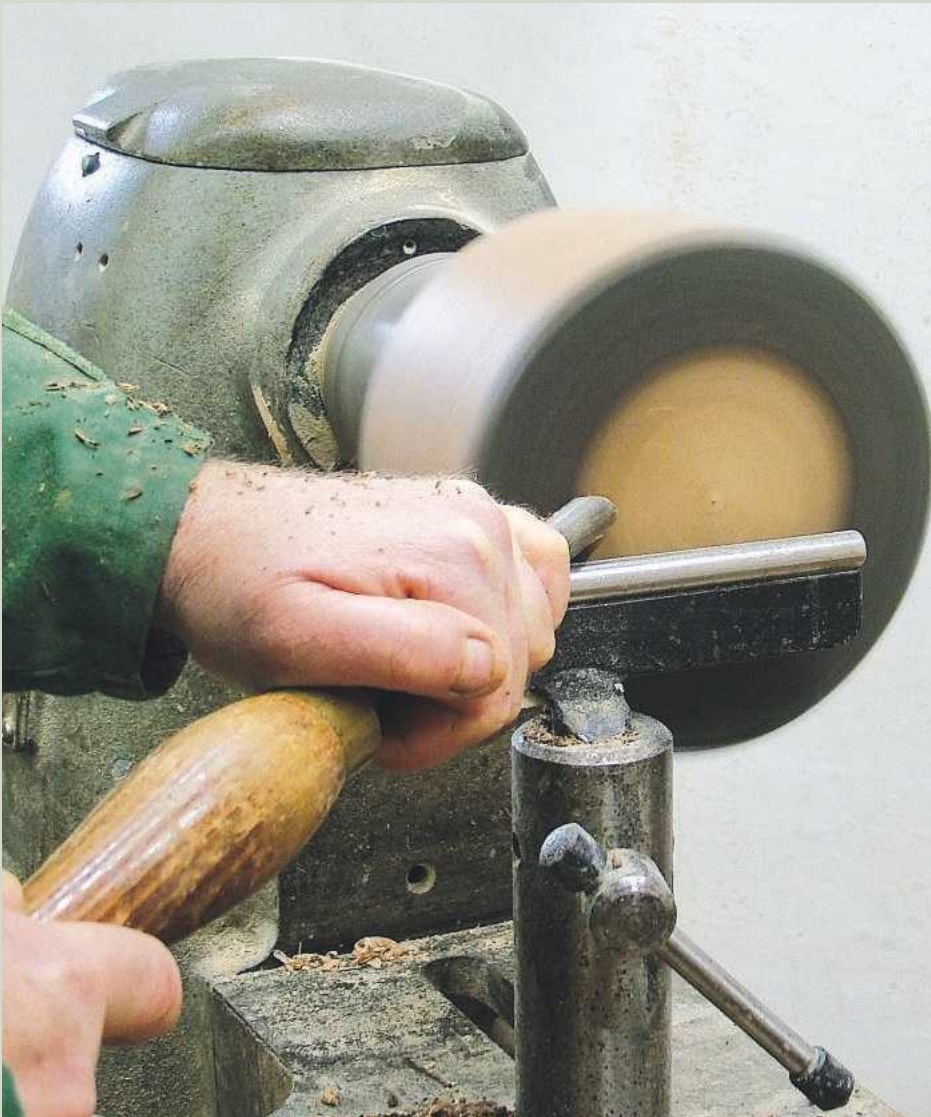
2 Use a pull cut to flatten the base...
