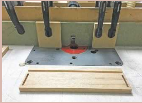
16 All drawers were made using solid ash, then glued with solid wood splines. Here the router table is being used to create the grooves
