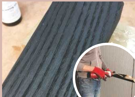
22 The legs are scorched using a blow torch, then ebonised
