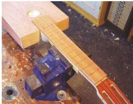
41 A dry fit of the fingerboard...
