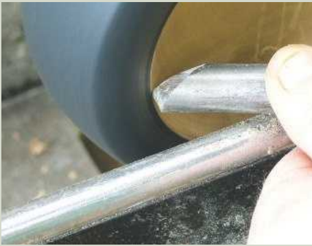
16 To increase steepness of cut, the bevel must point in this direction
