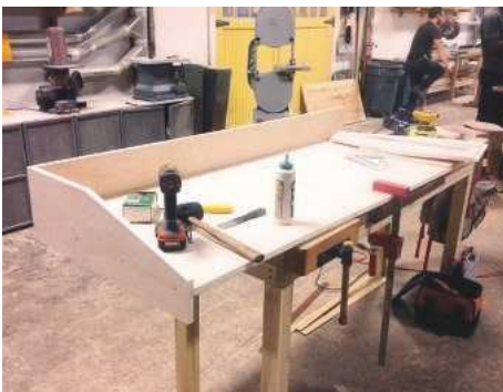
10 Repeat for the sides, ensuring that the backs of the sides capture the rear piece's edges
