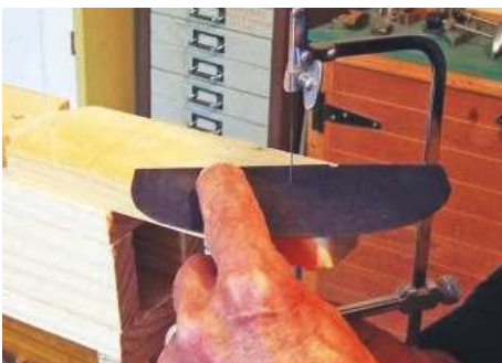
56 Fretting out the pickguard
