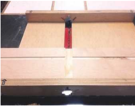
3 A sled allows you to make cross-cuts on the table saw while protecting against kickback – never make cross-cuts on a table saw without one! Here you can also see the 41mm groove
