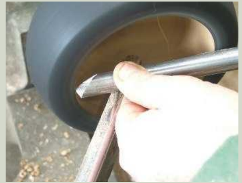
18 To undercut, ensure the bevel points under the rim
