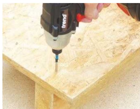
Any impact driver is best suited to jobs such as decking installation, laying OSB or plywood sheets...
