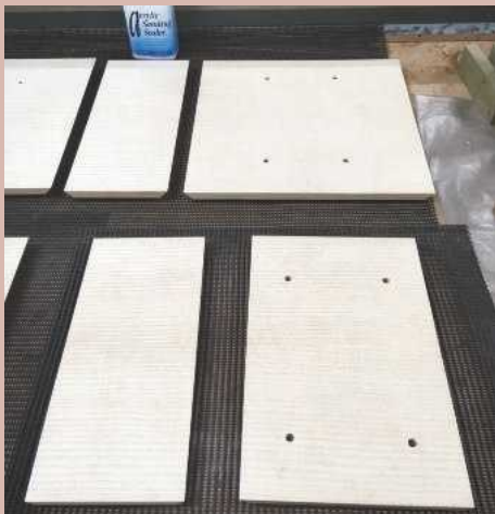
9 The veneered boards were cut to size with mitres. Each board allowed for a continual flow of grain across the top and sides. Next, fixing holes for joining the boxes were drilled in and threaded inserts added
