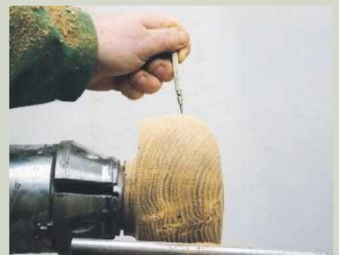
8 Try to ensure the widest part of the bowl isn't situated midway between base and rim
