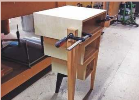
21 Test fitting domino joints on the legs prior to scorching
