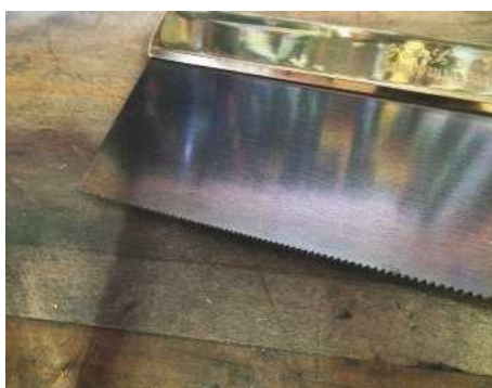
12 Modern dovetail saws tend to have finer teeth at the tip to prevent 'grab'
