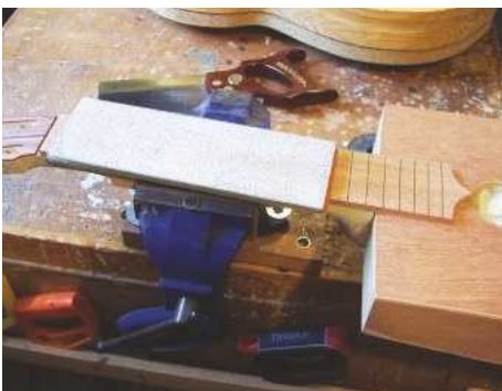
43 ... and levelled with a glass sanding stick
