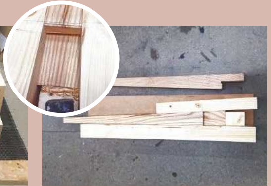
20 Cutting the tapered legs, and making a jig for the router in order to create a square notch at the correct depth
