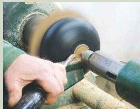
29 Reverse chuck the bowl in order to remove the chucking spigot
