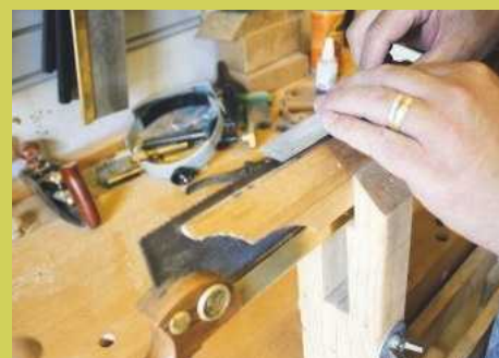
3 A light topping will indicate where the work most needs doing
