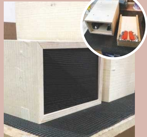
11 A test drawer in MDF was made in order to try out the final drawer front design. This was useful to see how it all looked and to check that all worked as it should in terms of the runners
