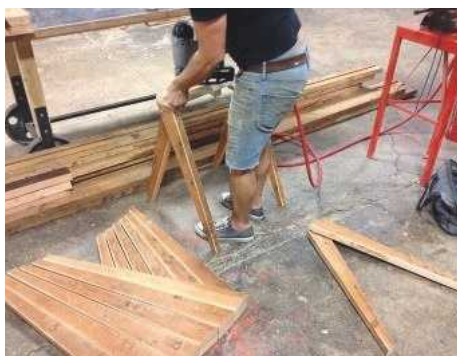
17 Secure the top plate to the legs with glue and a few brads; this will hold it steady while you drive in the screws
