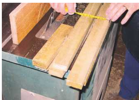
2 For ease of trenching later on, the rails should all be cut to the same width
