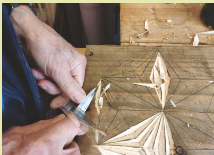
9 You'll be left with the final two limbs, where the chord intersects the outer circle
