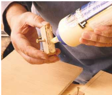
14 Adhesive is applied to pre-drilled and countersunk blocks, which are positioned along the line
