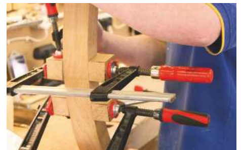
24 An array of clamps holds components in place while the glue sets
