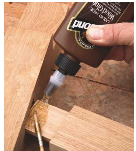
10 Modern solvent-treated hide glue doesn't require heating and therefore allows a much longer open time
