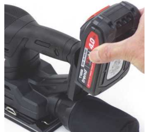
With 2Ah battery fitted, the 1/4 sheet sander is the heaviest of the three, weighing 1.8kg overall
