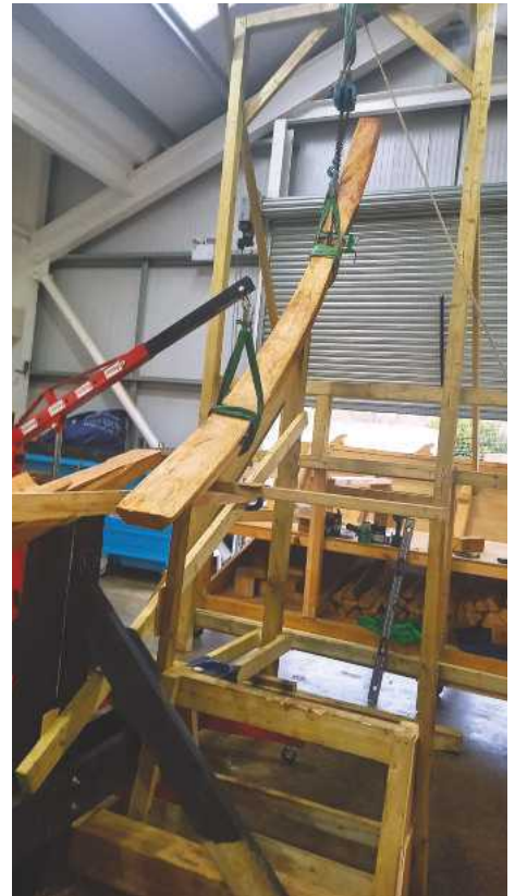
Initial lifting of the stern-post
