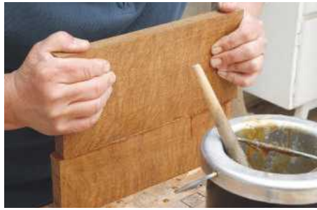
20 Instead of clamping, the glued edges are rubbed together for a few seconds until the joint grabs
