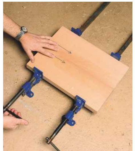
18 Boards are clamped edge-to-edge while the glue sets
