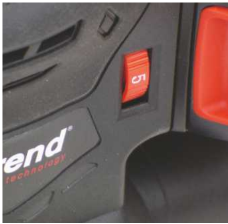
The random orbital sander features variable speed, which is easy to adjust via a thumb dial towards the rear of the body
