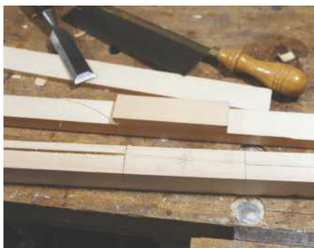
17 Saw the centre section square and remove any waste
