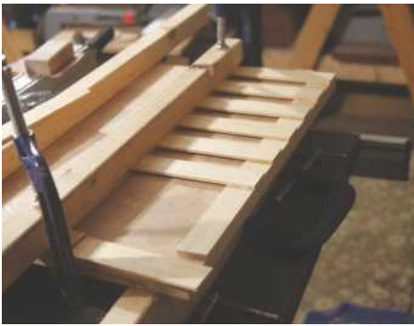
22 Make a simple jig to help with this stage
