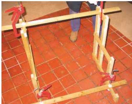
8 Cramp on a couple of slats as shown to help you space the end frames correctly
