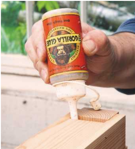
4 Polyurethane glues are particularly useful for joints with gaps as well as where a lot of seasonal wood movement is expected
