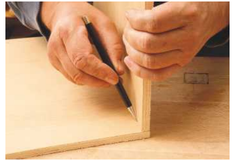
13 For a screwed and glued joint, using a pencil, begin by marking the position of one board against the other
