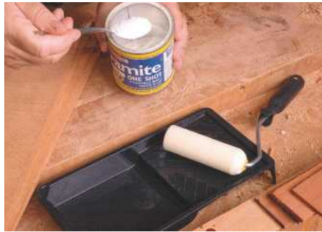
5 Glues made from powdered synthetic resin are good for spreading over large areas
