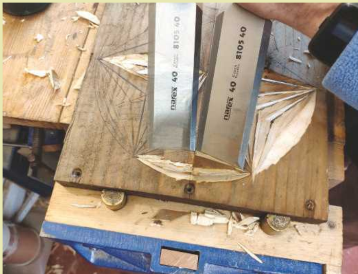
10 To finish this quadrant, you'll need to return to the straight blade
