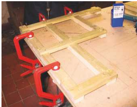
7 Drill clearance holes in the rails and drive in two fixing screws per joint
