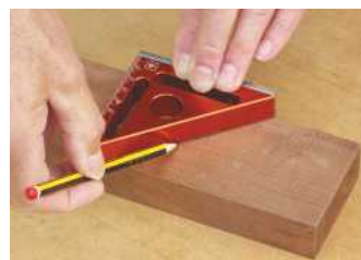
The hypotenuse is unmagnetised and can be used for marking out 45° mitres, or adjusting fences
