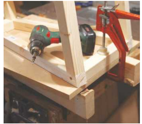
3 Ensure all lower rails line up with one another
