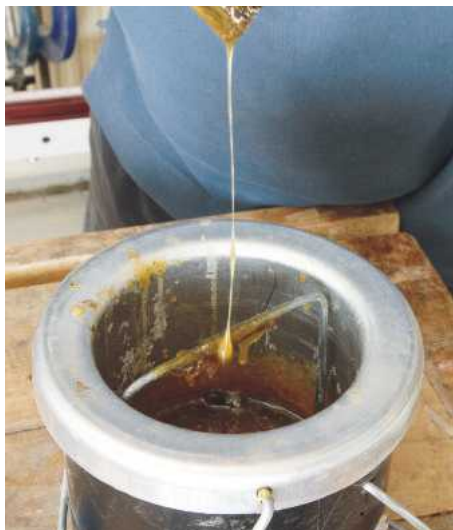
9 Pearl glue mixed with water is heated until a thin gel is formed, which thickens within a few seconds of cooling
