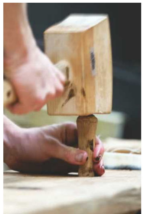
A treenail is hammered in to join the first two parts of the keel on the replica ship
