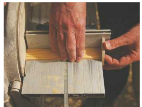
21 Using off-the-shelf timber, produce 24 identical pieces for the sails
