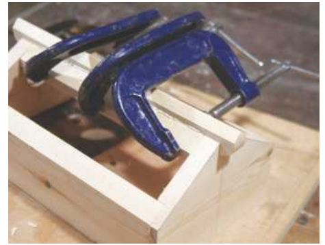
15 Note slope to secure the roof
