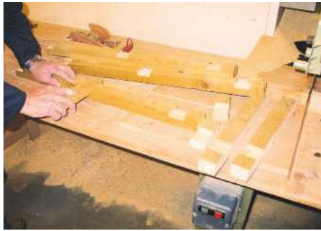
4 Check the fit of the rails in the leg housing joints, easing them if necessary
