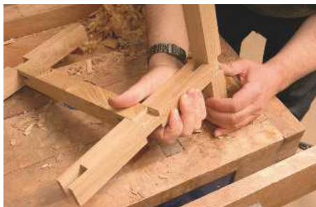
23 Rehearse fitting joints dry before gluing them in place. However, it's best not to fit fully as they may be damaged when pulled apart
