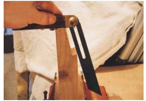
6 Using a bevel, check your cuts are true. Practice makes perfect here!
