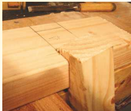
3 Lay the leg into the housing to achieve a tight fit, then draw around it
