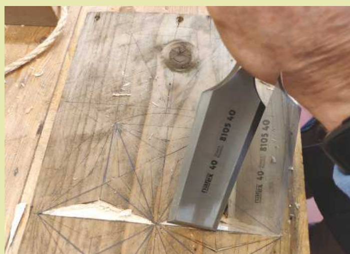
7 To remove the chip, repeat this process along the diamond's centreline
