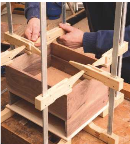
25 Sometimes a large number of clamps is necessary to pull evenly in both directions
