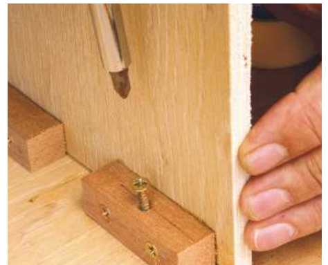
15 With glue applied to all contact surfaces, the joint is screwed together
