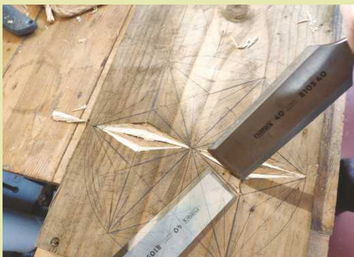
8 The next level to work on is the same triangular shape as before, taking two opposing 45° chisel cuts to remove the chip
