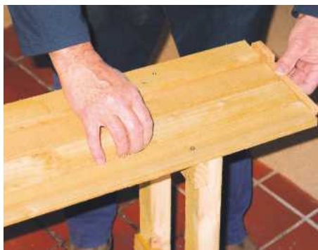
11 Space the intermediate slats by eye and use an offcut to make sure the ends are aligned
