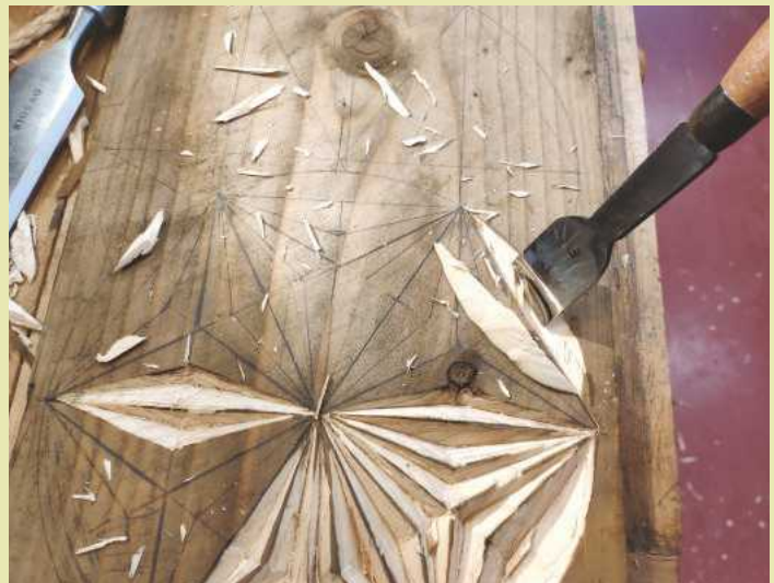
11 If you have a suitable gouge, the curve can be established more quickly with a series of slicing cuts along the arc
