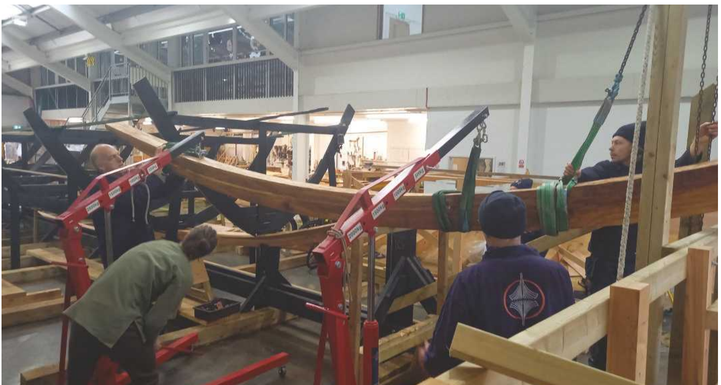
Partway through lifting the stern-post into place
