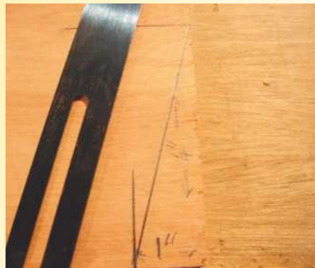
1 To make your bevel board, mark out on a scrap of timber. Set the bevel as your guideout
