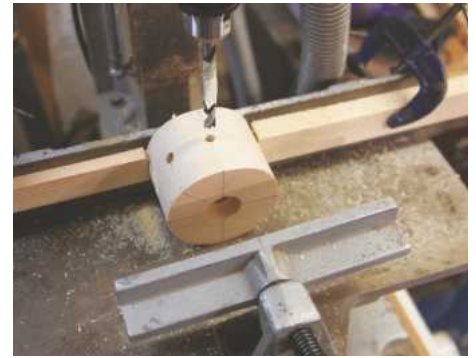
24 Ensure the drill bit is pointing towards the hub's centre
