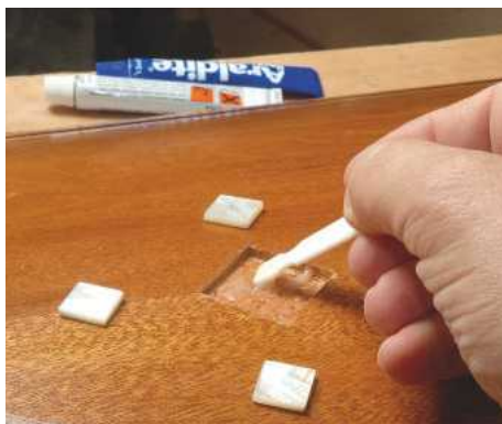
7 Two-part epoxy resins are ideal for fitting small decorative features or for embedding metal reinforcements into joints
