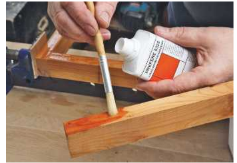
6 Resins with a separate liquid hardener are immensely strong for close-fitting joints where a long open time is required
