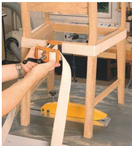
26 Awkward and irregular shapes, such as this chair seat, can be pulled together using a strap clamp
