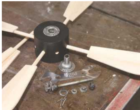
25 Paint the hub prior to fitting the feather piece
