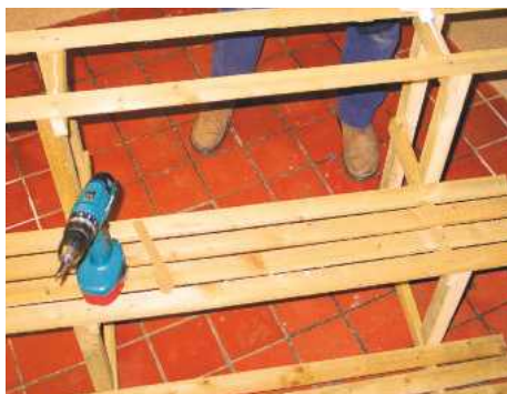
10 Add the inner slats to each level, gluing and screwing them on as before
