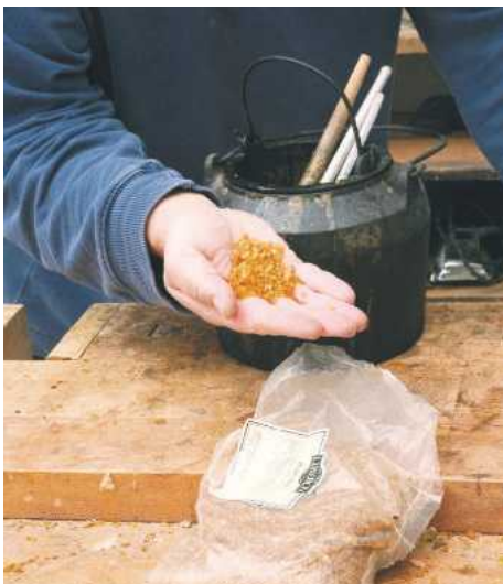
8 Traditionally used by all furniture makers, pearl glue – also known as hide or scotch glue – is now only used for antique repairs and making musical instruments
