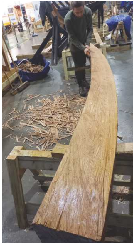
Alec Newland completing the final profile of the inner face of the stern
