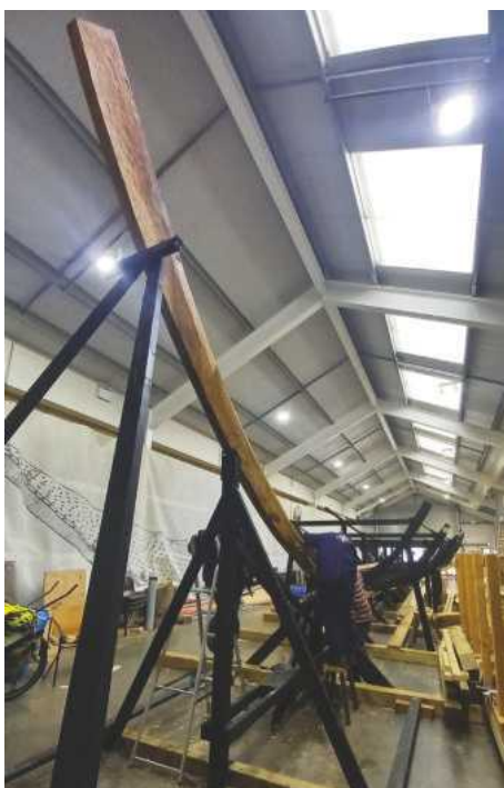
Stern-post once erected
