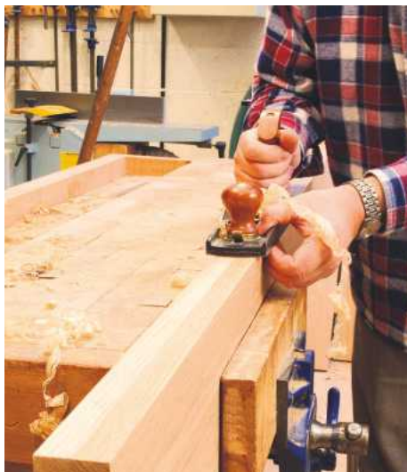
16 When preparing an edge joint, the two boards are clamped face-to-face, then the edges planed as a pair
