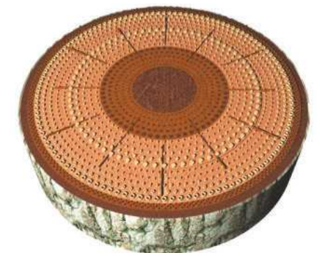
A model showing a slice through a ring-porous tree, such as deciduous oak
