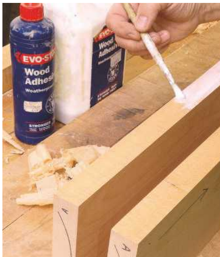
17 Planed edges are evenly brushed with a layer of white PVA-type adhesive
