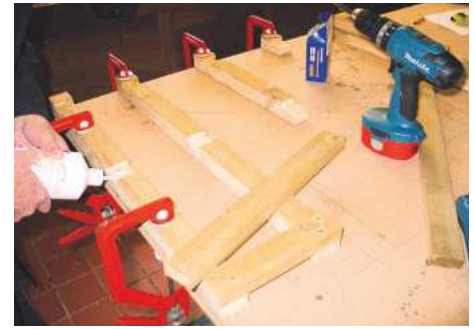
6 With all the legs cramped in place, apply plenty of glue and begin to fix the rails
