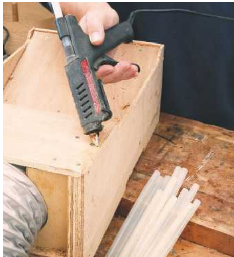
11 Hot-melt glue sticks are handy for temporary fixings and sealing gaps, such as in a dust extractor, as shown here
