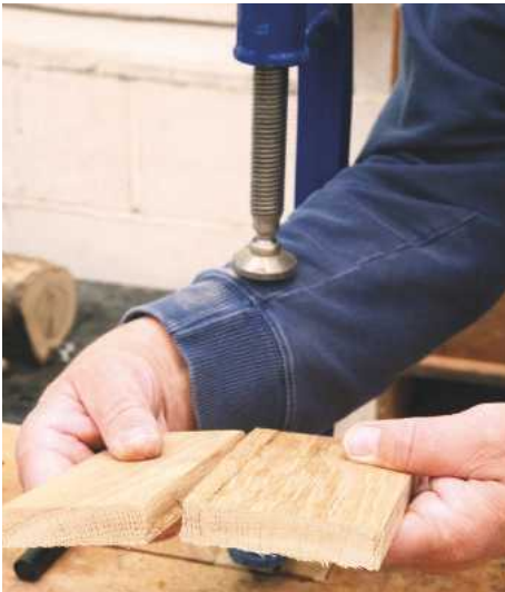
1 Oak boards, which were glued edge-to-edge, then snapped using clamps. The break occurred 10mm to the left of the glue line, which shows that the glue was clearly stronger than the wood
