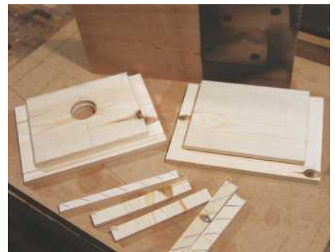
9 Cut the rebates, allowing for a slope on the lower front edge
