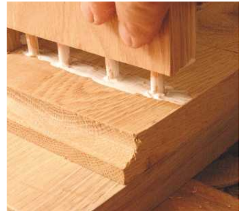
21 Dowels are versatile components for making simple glued-up joints and don't require any specialised knowledge or equipment
