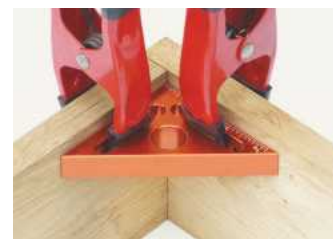
A couple of mini spring cramps do the job, though probably not quite as well as dedicated ones
