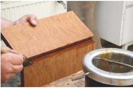
19 Traditional edge joints, made with hide glue, need to be quickly worked and don't require clamps
