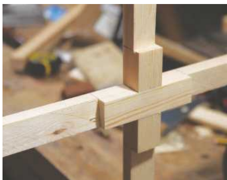
20 Note how the bevels all follow round the spars
