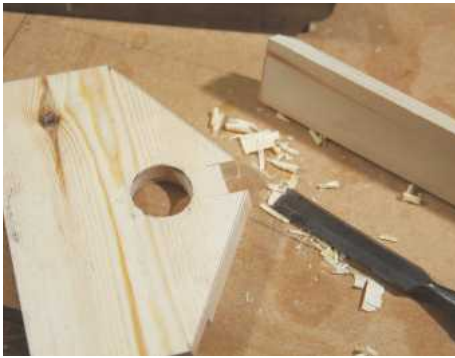
13 Chisel a notch for the roof ridge piece
