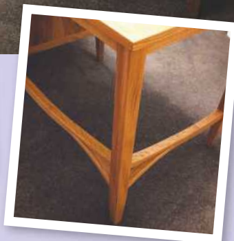
Steam-bent oak rails, which split to create a strengthening brace
