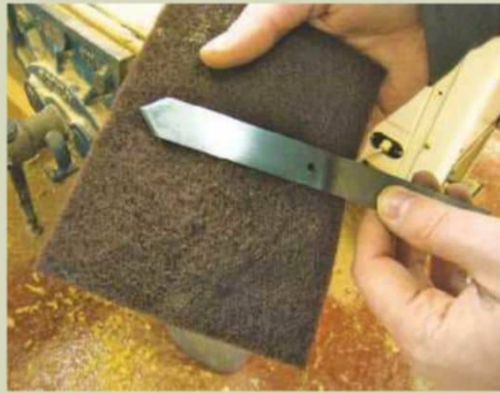
8 The process left the metal black, which I proceeded to rub off using a Hermes Webrax pad
