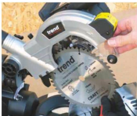
Raise the guard, remove the blade, reverse the process and you're ready for action
