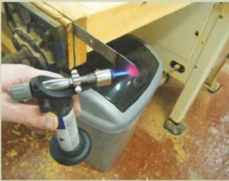
7 I used a blowtorch to heat and harden the blade steel, which was clamped in a vice
