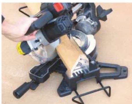
The MS184 is a single bevel saw, with the saw head tilting to the left
