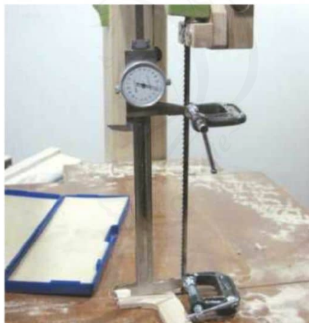
A simple trick for measuring the strain on the blade is to clamp a calliper to it
