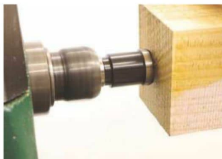
Releasing tailstock pressure allows the teeth to disengage with the lathe running
