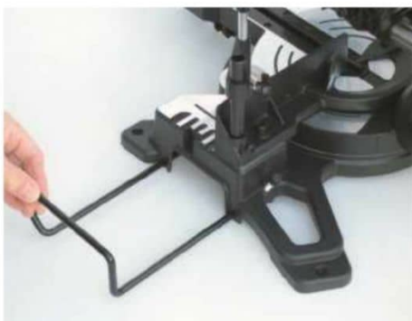
Support arms, provided at each end of the table, are extended outwards by slackening off thumbscrews at the back
