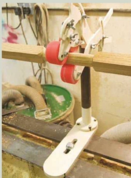
A good spindle steady like this Oneway model from Hope Woodturning is absolutely essential
