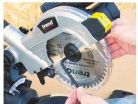
... before slackening off the blade retaining bolt and arbor using the hex key provided
