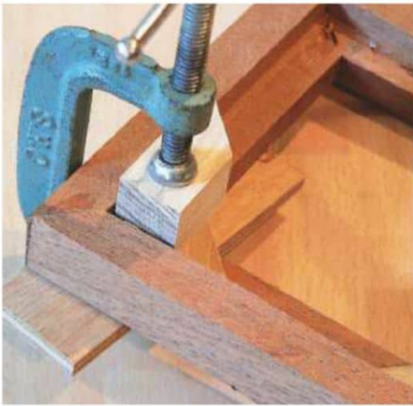
7 The mitred corners need to be reinforced with plywood triangles
