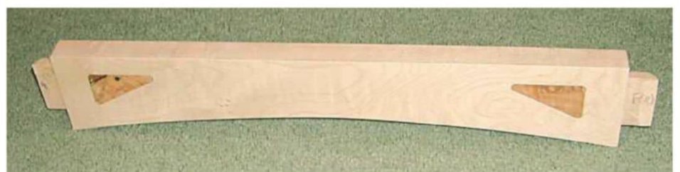
6 Leftover spalted beech was used to create inlays on the front rail – a great decorative feature
