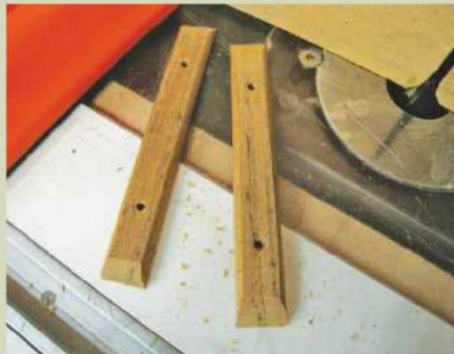
11 I rounded over the edges of both sides of the handle on a router table
