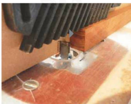
3 ... and the same depth, in order to accept the shade parchment
