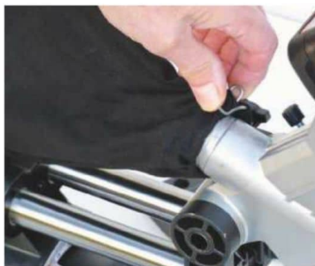
A fabric dust bag is provided, which clips over the port on the saw head
