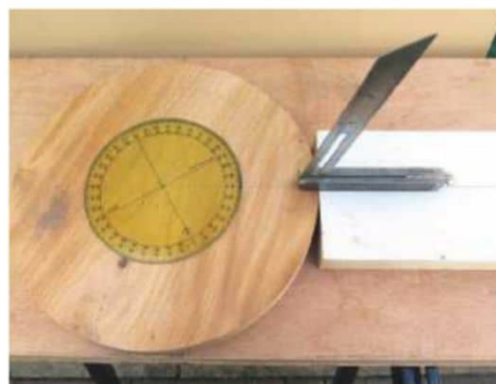
5 Marking out leg positions using a protractor
