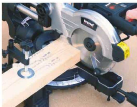
The MS184 effortlessly sliced through 45mm softwood...
