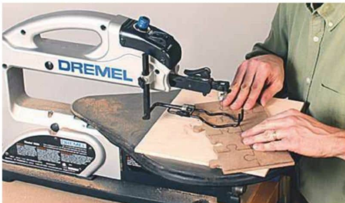
13 Cutting jigsaw pieces using a scrollsaw
