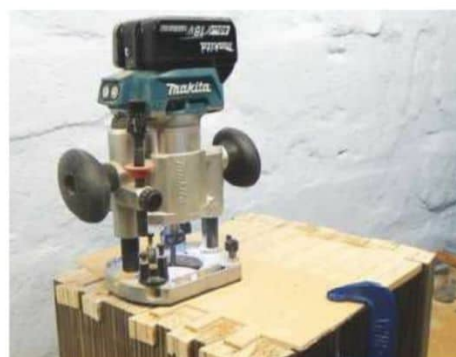
3 Using the Makita DRT50 to surface skim my novel dovetail joints
