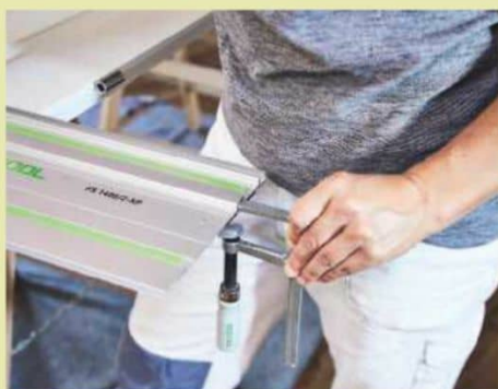
4 Take the guide rail and position using one fastening clamp in the lower groove
