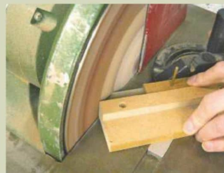
6 I roughly cut the point at the end of the blade using a disc sander and mitre gauge
