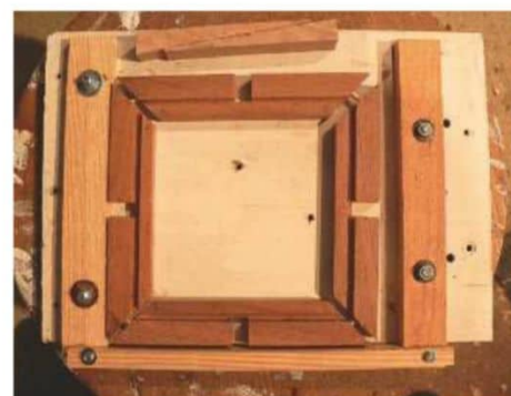
6 The pieces for the lamp's top frame can then be glued together and clamped around the block
