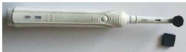
Colin's ingenious electric toothbrush sander with polishing attachment
