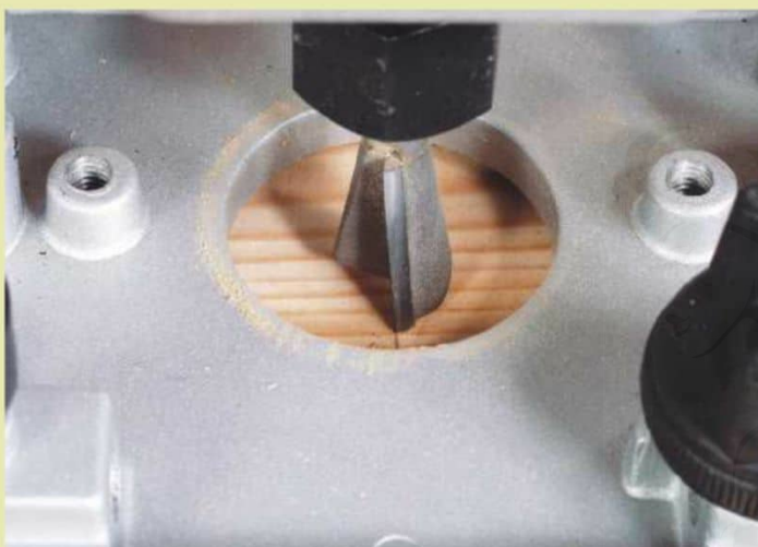
3 Fit your router with a dovetail cutter. The diameter should be reasonably close to the shelf member's thickness. To centralise the router on the line, unplug it, stand it on the board and plunge the cutter down to touch the surface. Turn the cutter by hand and move the router until both cutter faces are exactly on the line
