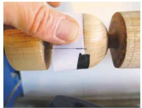
9 A strip of paper is used to measure the circumference of a turned ball
