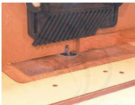
1 Run a groove down the outside edge of the rear vertical; this will house the electrical wire
