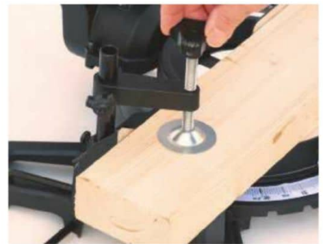
The arm of the hold-down slides on a steel pillar and is locked with a thumbscrew, while the workpiece is held tight with a steel clamp
