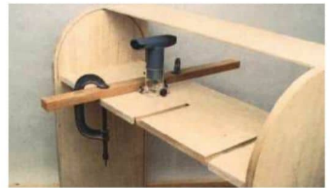
8 A small plunging router can radically simplify life with staged carcass construction
