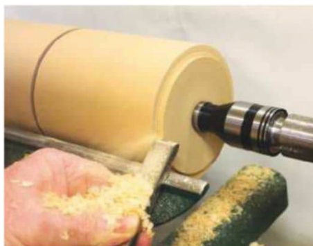
The Revolving Stebcentre provides excellent tailstock support
