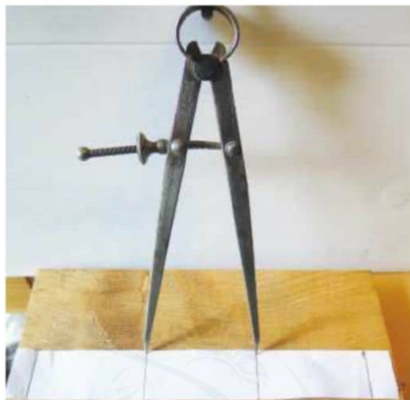
10 Dividing the circumference by three using a pair of callipers
