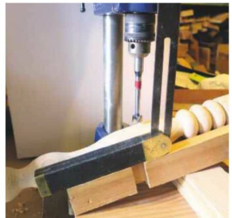
11 A 15mm Forstner bit held in the angled cradle jig
