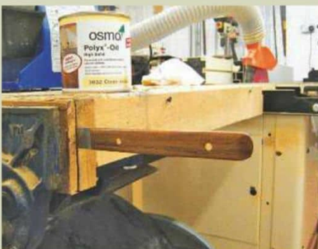
13 With the blade end clamped in a vice, I applied a Polyx oil finish
