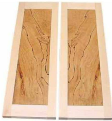
3 10 coats of Rustin's plastic coating gave the doors their attractive finish, and some additional strength to boot
