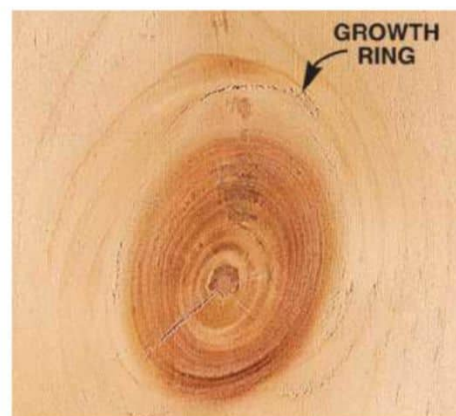
An intergrown knot is the base of a living branch within a tree, which is surrounded by a halo of circular growth rings. An intergrown knot is also called a 'tight' knot because it's tightly bound to the wood around it
