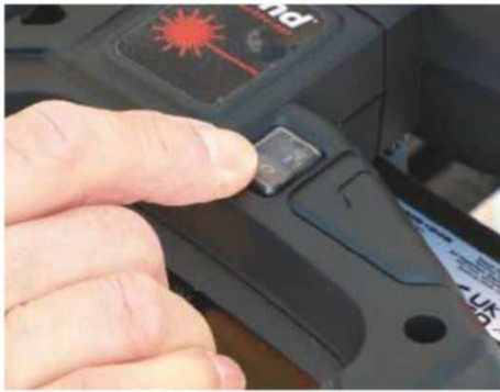
A small rocker switch located on top of the handle is shrouded against dust
