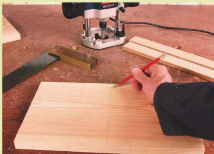
2 Unless you want the dovetail to show through on the front of the joint, you need to mark a point where the housing will stop. This should be 5-10mm from the edge
