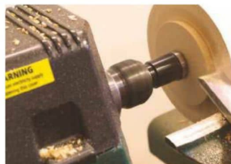
Using a skew chisel to form a dovetail spigot. The drive is very secure
