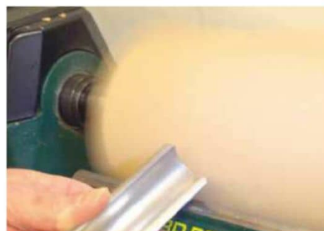
The Stebcentre provides plenty of grip to drive this piece of 100 x 100mm ash
