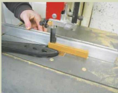
2 After planing the iroko down to correct thickness, I dimensioned the piece in half on a bandsaw
