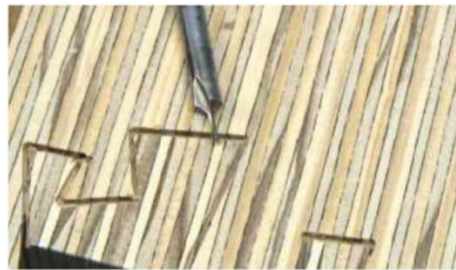
7 Surgical precision and great concentration are required to rout these narrow groove joint highlights
