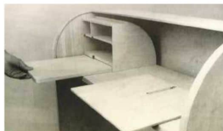
9 The main carcass is glued and clamped, then subsequent members housed in
