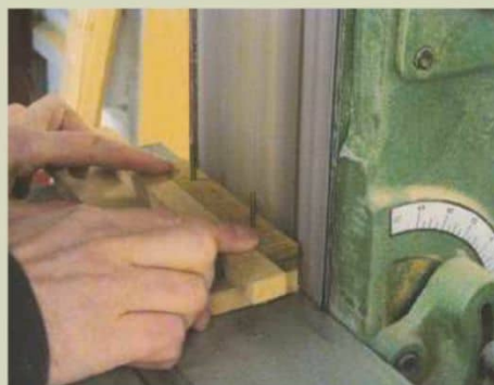
5 Held together by rods, this was placed on the jig and the metal sanded back to the handles
