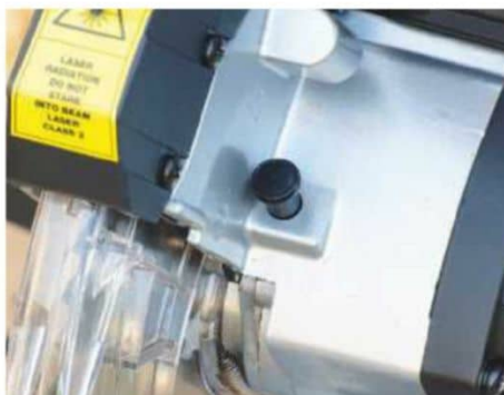
With the saw head raised, you depress a spindle lock button on the motor casing...
