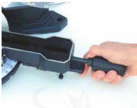
... but this didn't pose a problem, and angle selection is effortless using the spring-loaded lower lever
