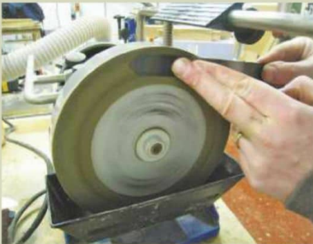
10 ... and used the side of the stone to initially polish the blade's reverse
