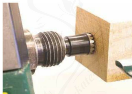
Timber in place. Pressure from the tailstock engages the teeth
