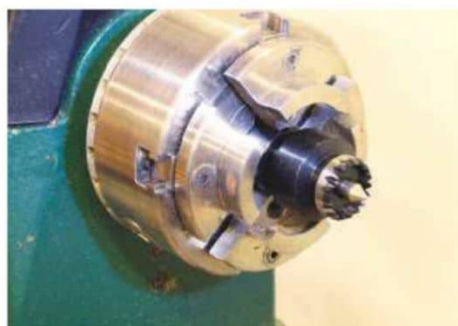
The jaws must close on the flats as opposed to the rounded corners
