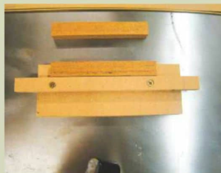
3 Using this piece as a spacer, I made an MDF jig to hold everything together while I machined the metal
