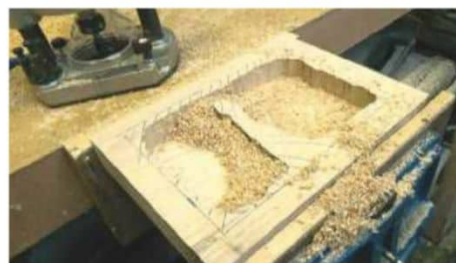
11 Over three times the runtime using my fast plunge method to trench a 20mm deep mortise. After 12 minutes, more stock is removed with a staggering three-quarters' power remaining
