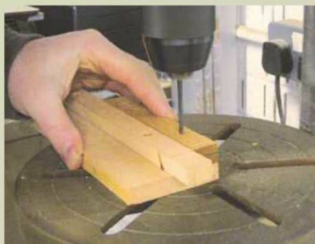
4 With the metal and wood piece held together, I drilled holes for the brass rods
