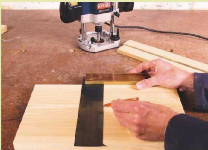
1 Start by marking out the position of your joint on the side panel. Just use a single line to mark the joint's centre
