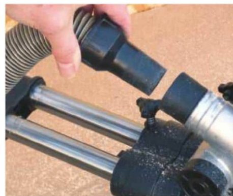
As with most mitre saws, this only collects some of the waste when cutting – it's much more efficient to hook up a vacuum extractor
