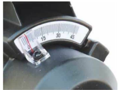
A pointer at the front of the pivot mechanism is easy to read and can be calibrated to zero
