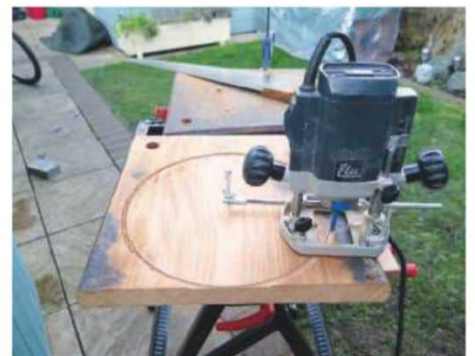
3 Using the router to create a circular top
