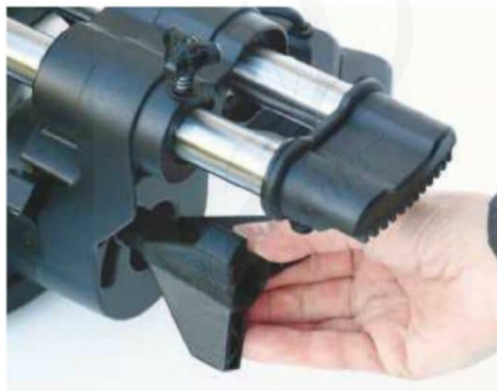
For making bevel cuts, you tilt the blade by slackening off a hefty triangular knob located at the rear
