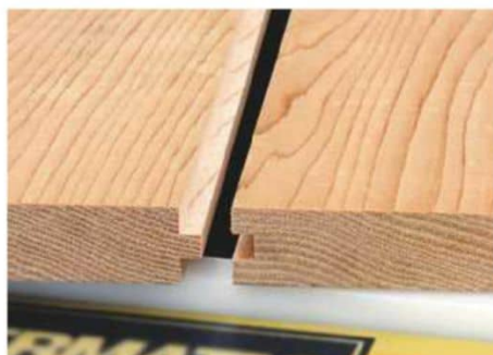
The tongue & groove joint adds strength and exact alignment
