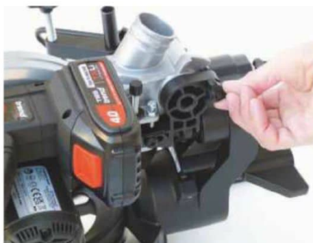
For transport or storage, the head is locked down with a pin
