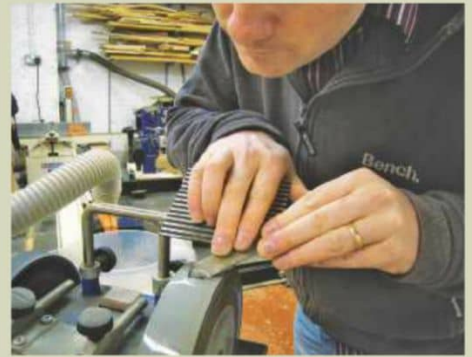
9 I ground an edge into the blade with a general mounting jig set at 25° ...
