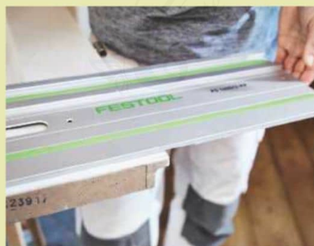
5 Make fine adjustments to the guide rail. Align it so that the splinter guard is positioned exactly on the mark
