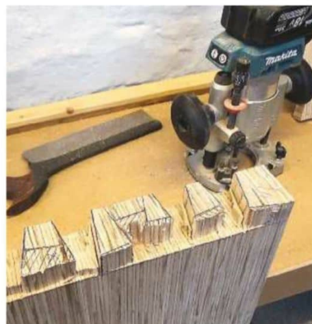
4 Surgical precision: the compact Makita DRT50 allows unconventional fast and accurate waste removal on the same novel dovetail joints
