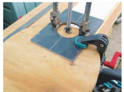
6 Angled drill at 12° with sawtooth bit
