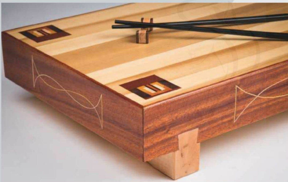
'Floating Top Side Table' – the floating illusion is created using copper pieces set under the top. Delicate inlay surrounds the edges and follows the legs' graceful curves. The table top has been book-ended to create a stunning image. Made using cherry, walnut, maple and exotic hardwoods – 457 × 457 × 635mm
