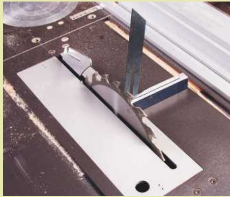
13 Transfer this angle setting to your table saw – PLEASE NOTE THAT THE CROWN GUARD HAS BEEN REMOVED FOR CLARITY
