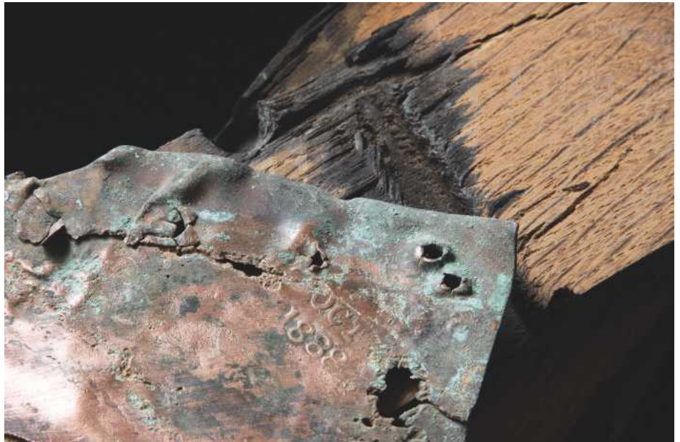
Copper and oak: much of the Victory material is tattooed and scarred with use, with everything from paint and iron stains to bolt holes and stamps; the date on this plating identifies it as part of the last coppering of Victory's hull
