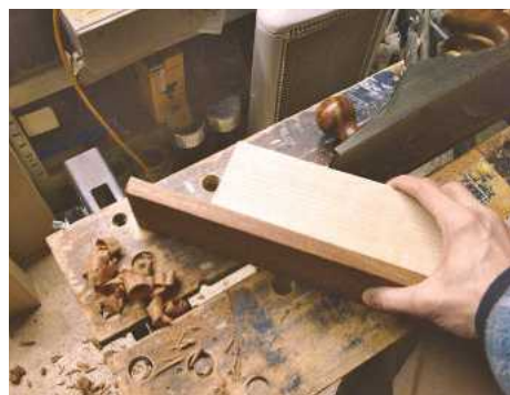
3 The laminae of ash and sapele were fixed together using Gorilla glue, which I find reliable and easy to use
