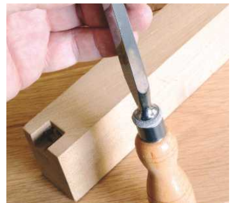
4 A chisel's square sides cause it to line up accurately when cutting rectangular holes, such as the small rebate shown here
