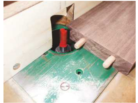
3 Cutting rebates for the box bottom using a router table
