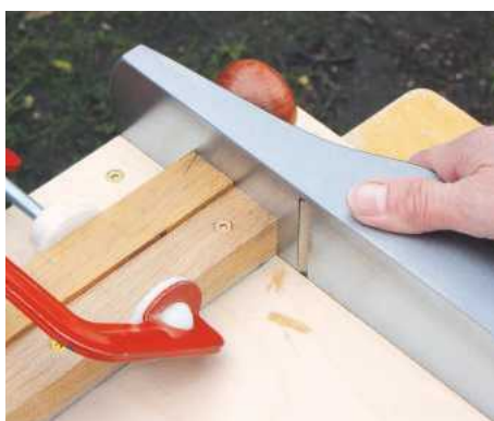
8 Before use, trim the end of the planing stop. Cramp a backing piece to this in order to prevent splintering
