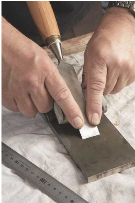
13 The chisel and gouge are guided using both hands; this provides a balanced level support without any danger of rocking, and the blade slides up and down on a fine polishing stone
