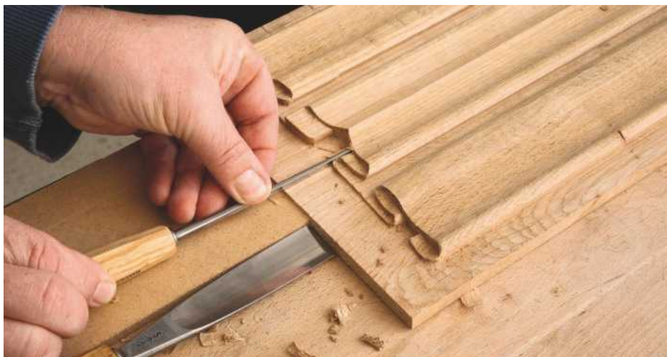
19 Traditional 'linen-fold' carving as a classic illusion, shaped with planes and gouges to give the appearance of folded cloth
