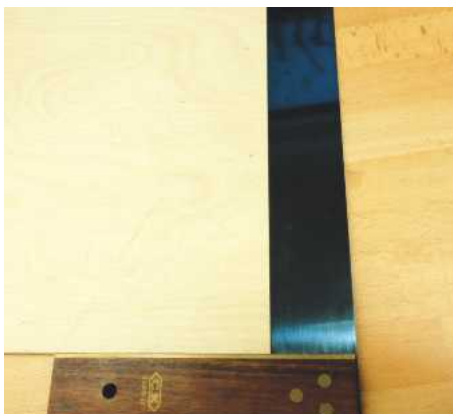
The proof's in the pudding: using the Rail Square, it's possible to achieve an accurate right-angled cut
