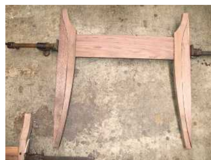
12 Clamping up; note use of offcuts to assist with curves
