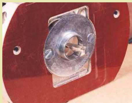
9 Fit the router with guide bush and dovetail cutter
