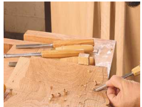
18 Moving on to shallow relief carving, these floral patterns for a chair back are developed using saws and gouges
