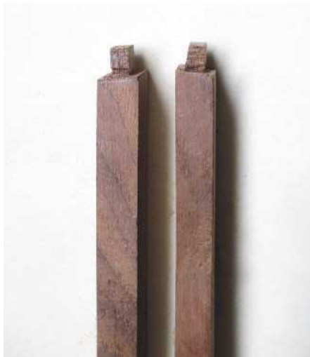
4 A dowel hole on the leg with transfer marking cap fitted...
