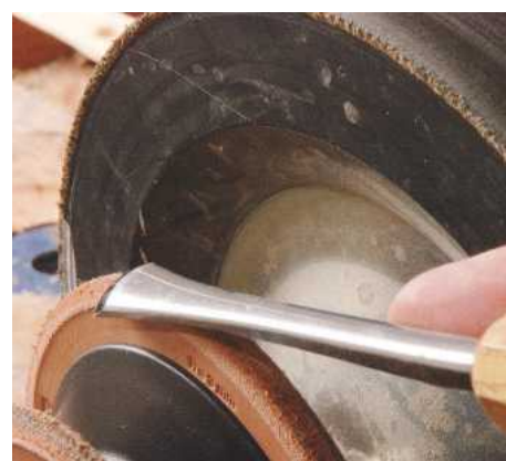
25 Leather wheels aid honing, especially on the inside of a carving gouge
