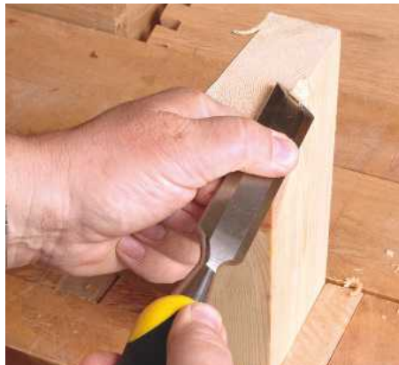
1 A basic plastic-handled chisel is used to pare a chamfer on the end of a soft pine board
