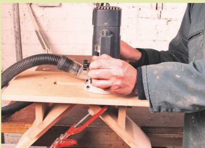
7 Insert the setting bar through the jig and line up on the marked lines
