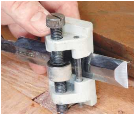
12 Clamping in a 'honing guide' allows a chisel edge to be finely honed to an accurate angle
