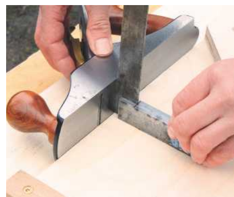
9 It's important that the sole of the plane is square to the top board – check this using a square
