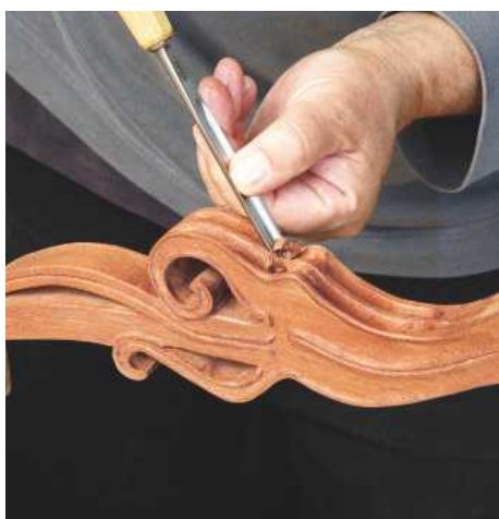
20 Three-dimensional patterns carved in furniture frame work require the maker to be very aware of grain direction in order to avoid tearing the wood
