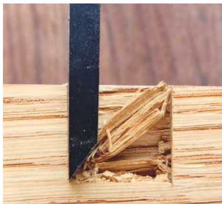
3 In chopping mode, this square-edged chisel acts as a knife, severing fibres, as well as a wedge, forcing waste away from the newly-cut surface
