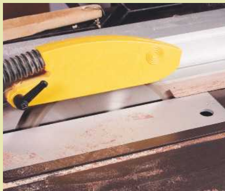
15 To adjust the fit, lay the timber on its side and with the blade still tilted, take shaving cuts off the bottom until the piece just taps into the dovetail sockets with a light hammer
