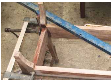
13 A diagonal clamp helps to keep things square
