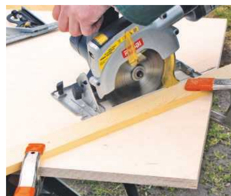
6 Cut a right-angled triangle to form the mitre shooting board. Plane up the sawn edge
