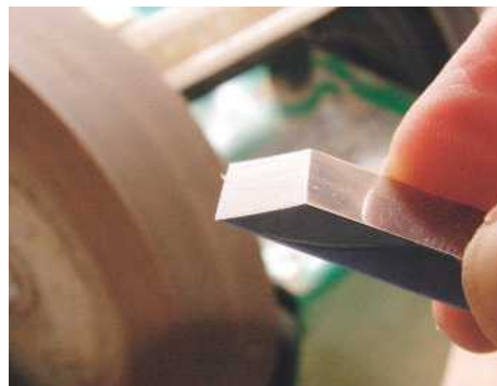
11 After wheel-grinding, the front bevel is slightly hollow and has a rough 'wire edge' on the very tip
