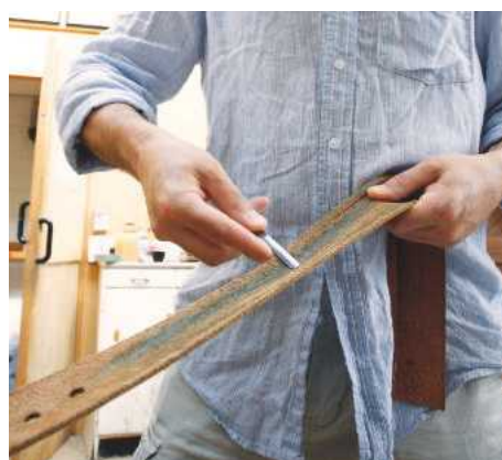
24 Gouges are stropped on leather to ensure they keep a finely honed, curved edge
