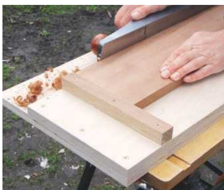
10 To shoot an edge, just hold the board against the stop and move the plane
