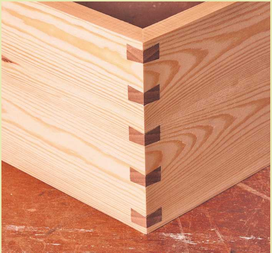
20 The completed spline dovetail joint ✂
