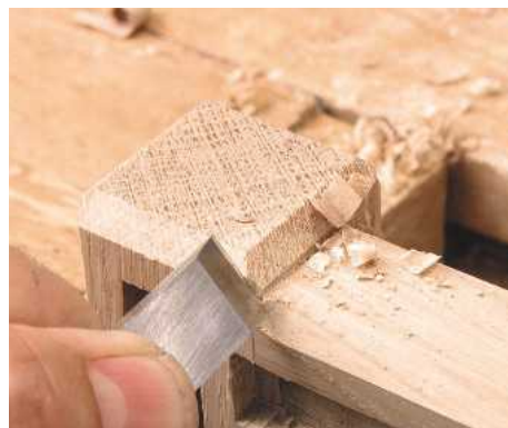
7 A fine-bladed chisel is used in paring mode to chamfer a corner from an oak post. Keeping the blade slightly tilted with the grain avoids catching and tearing it
