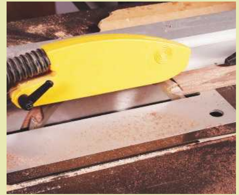
14 Set the rip fence a little wider than the base of the dovetail, and with all guards securely in place, rip down both sides of the timber to create your splines. Make up a long length and trim to size later
