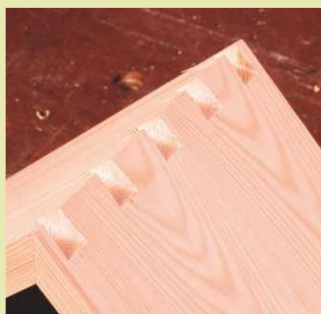
11 After machining, the joint should look something like this
