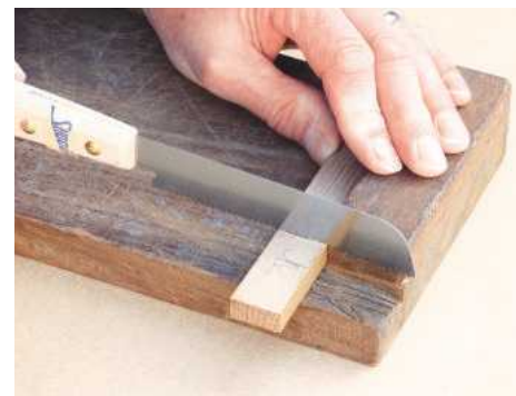
Blade length is 120mm on this fine, general purpose saw
