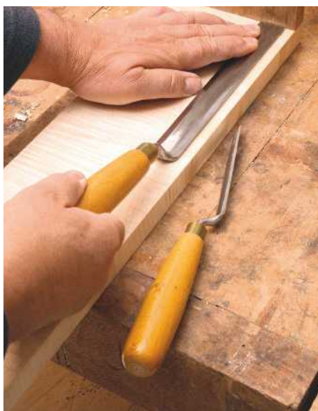
8 These cranked-shaft chisels reach into the parts that few other tools can, allowing you to create clean, flat internal corners of joints
