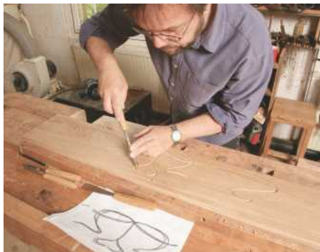
17 Still working in two dimensions on a flat surface, gouges are used to develop a flowing linear pattern
