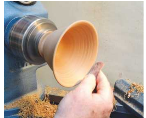
9 I sanded the bowl's rim, but left tool marks on the interior to imitate the appearance of clay
