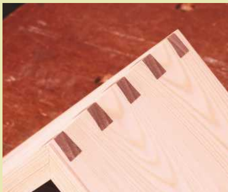
19 Finally, clean up the joint using a plane followed by fine abrasive paper
