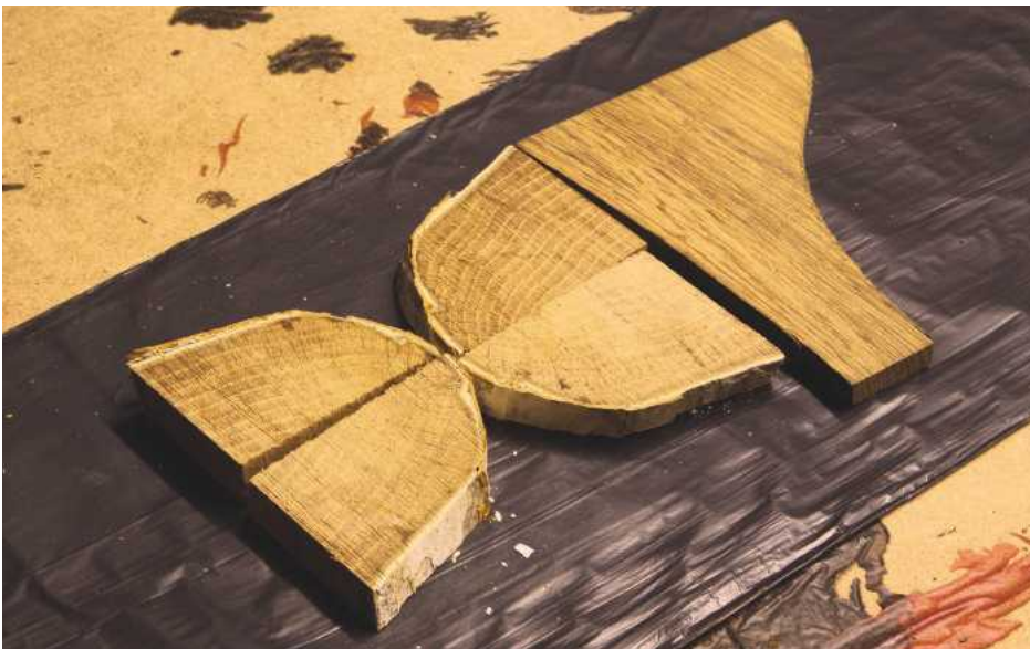
Small pieces of timber can be reconstituted by stitching them together with epoxy resin to create...
