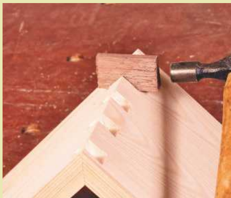
16 Cut the splines into short lengths, apply a little glue and gently drive into place using a hammer
