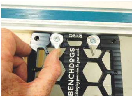
Aluminium cams lock the Rail Square in place
