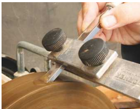
10 A chisel is accurately ground while held in a clamp on a water-cooled grinding wheel
