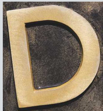
Resin metal is very fine-grained and behaves like solid metal – it's cool to the touch, workable with tools, polishes and abrasives, as well as being receptive to patination
