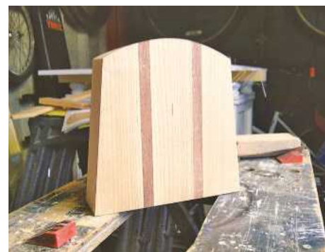
5 The top's corners were first sawn off and the curve perfected using a rasp, spokeshave and file
