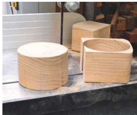
3 I cut out the bowl blank in the usual orientation – with grain running across the blank
