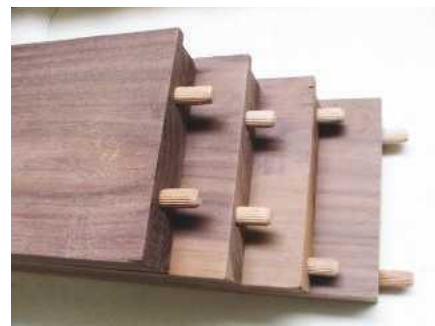
14 The four sides of the seat box – note staggered dowel positions to avoid structural weakness
