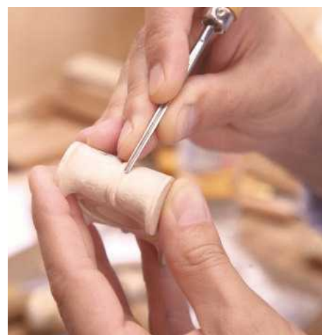
22 Very small gouges, such as this veiner, are used for finger-tip work when creating fine details
