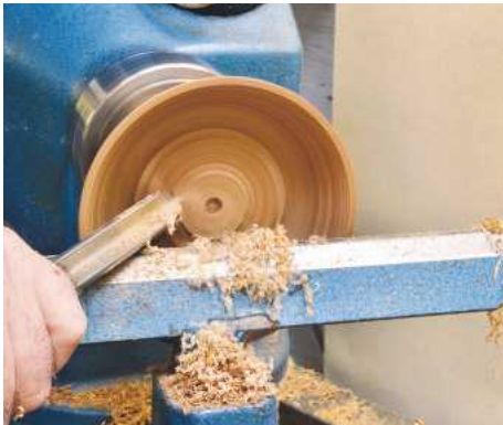
7 Hollowing out using a 13mm bowl gouge
