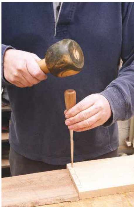
5 Shallow chopping using this bevel-sided chisel is used to mark out the baselines of sockets in preparation for cutting a joint
