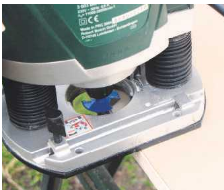
2 Rout a chamfer on the underside of the top board; this provides clearance for shavings and dust when planing
