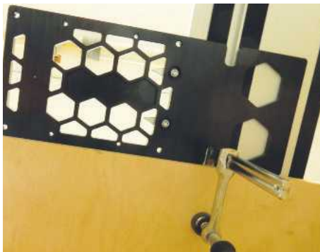
Standard rail clamps can still be used owing to cut-outs in the edges
