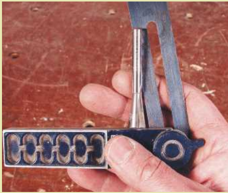
12 Remove the dovetail cutter from the router and set a sliding bevel to match its angle
