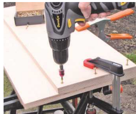
3 Drill and countersink the upper surface. Align both boards, then clamp and screw them together
