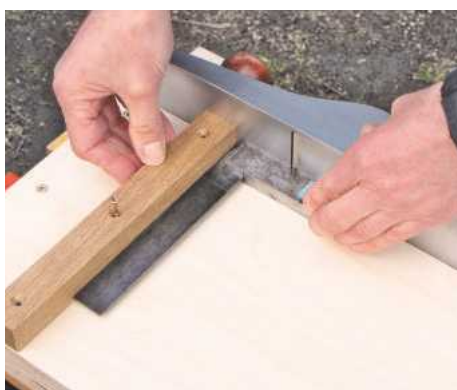
4 With the plane tight against the top, align the stop with a square. Glue and clamp before screwing
