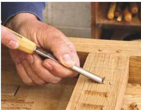
16 The gouge is a specially shaped type of chisel used to pare out grooves in carving work. Here, a traditional, simple pattern is made in oak from a series of matching parallel grooves
