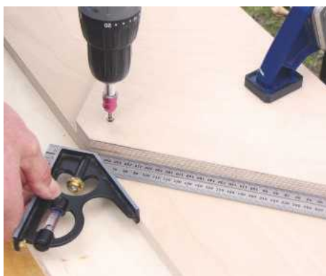
7 Ensure that the mitre board pivots slightly. Insert extra screws for accuracy, or clamp when shooting
