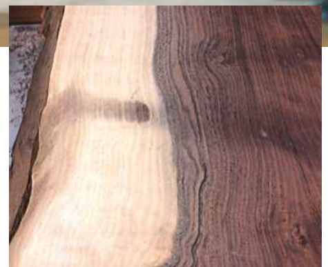
One of the more common drying problems is a dark area noted on dried, planed lumber, which is called 'sticker stain'
