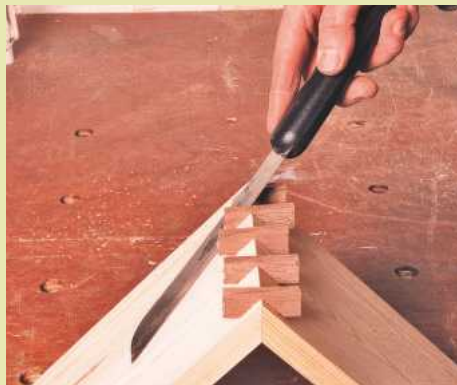
18 Trim off the waste using a flexible pull saw; this allows you to trim right up to the edge without damaging the workpiece
