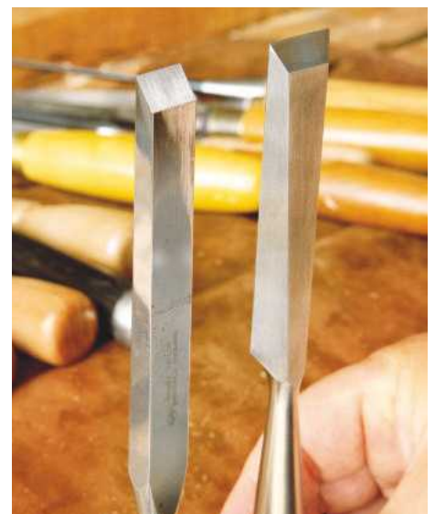
2 Two broad categories are the square-edged chisel (left) and bevel-edged chisel (right)
