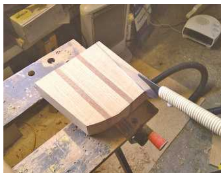
4 To remove the waste from the bevelled front and back, I used a saw followed by a plane to refine the shape
