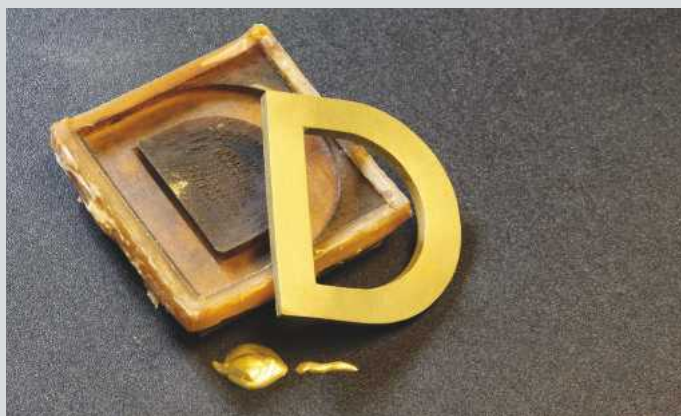
Using latex, it's easy to make moulds...
