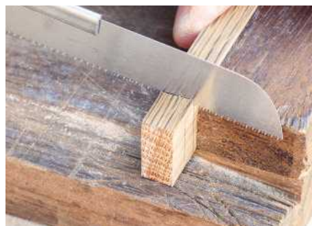
Featuring incredibly small teeth on its 110mm blade, the FLB100 is suitable for box or musical instrument making, as well as other detailed work
