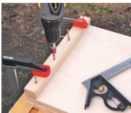
5 Screw and glue a similar hardwood batten underneath the jig; this will act as a bench stop
