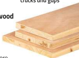
Blockboard is a panel consisting of a core of wooden strips between two layers of plywood
