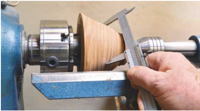
5 Mounted on a screw chuck, I turned the blank roughly to size and shaped it, transferring the diameters measured at different points
