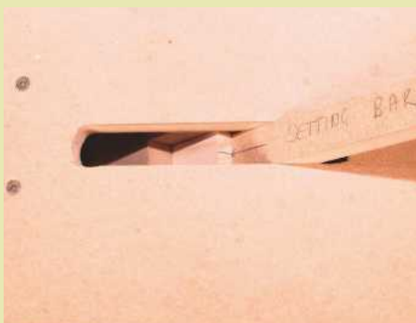
7 Insert the setting bar through the jig and line up on the marked lines
