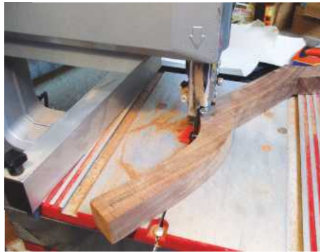
2 Cutting the back rail out using a bandsaw
