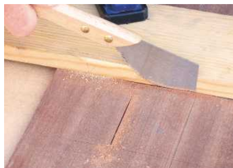
To achieve a really straight cut, it's best to run the saw against a guide batten, which is cramped or pinned to the workpiece
