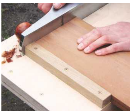
11 When it comes to trimming end-grain square, you should adjust the plane for a very fine cut
