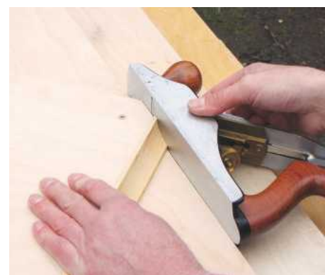
12 This is a multi-purpose jig, as trimming 45° mitres precisely is frequently necessary when making picture frames, for example
