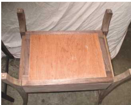
7 Fitting the lid – this will be upholstered later on
