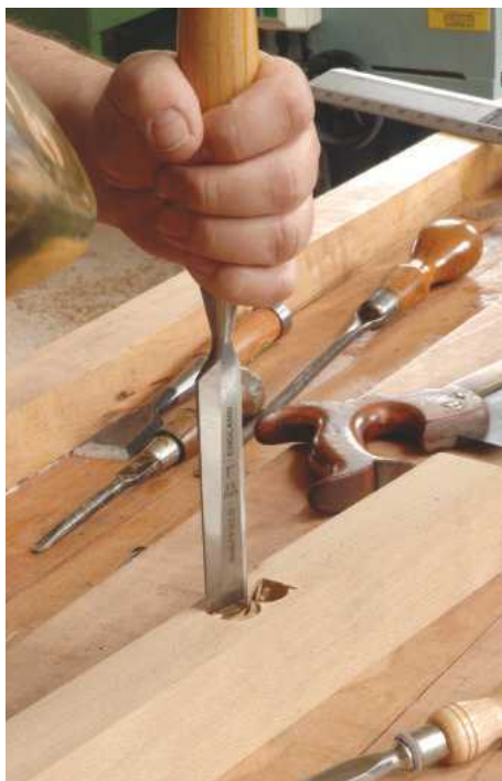
6 In a combination of chopping and paring, this bevel-sided chisel is used to convert a pair of drilled holes into a rectangular socket
