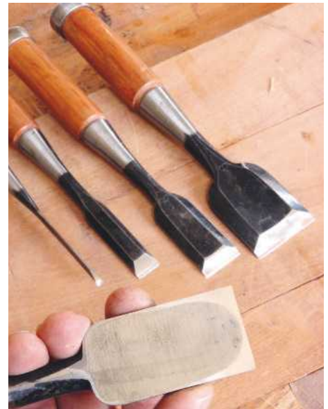
15 As Japanese chisels have hollow-ground backs, they can only be very finely re-ground; this avoids producing a distorted edge on the blade
