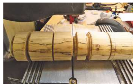
4 Using a bandsaw, cut the log according to the marks you made earlier
