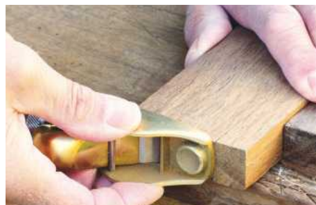
It's fantastic for shaping smaller items, adding chamfers or even planing end-grain
