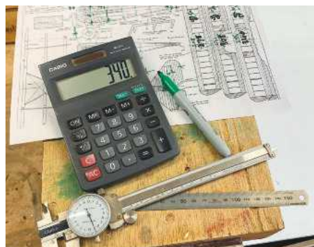
1 The plan I used gave no dimensions, and was slightly too small, so I began by measuring everything and multiplying by 1.5
