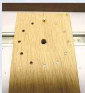
8 Insert brass rod pieces into the hour holes and gently hammer home. Carefully sand the face
