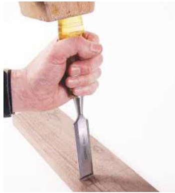
5 Remove waste from the mortises using a chisel and mallet. You'll need to work from both sides. Take shallow cuts and be careful not to damage the edges
