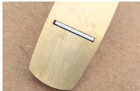
Due to its size, the mouth on this plane is non-adjustable and around 2.5mm wide
