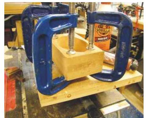
13 Glue the floor to the side of the hull
