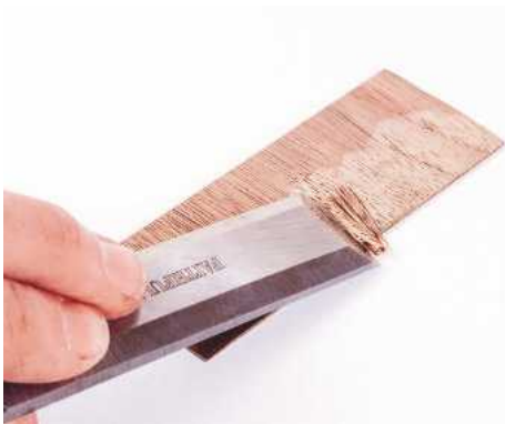
10 Cut a thin sliver of contrasting timber to make the wedges. Taper the end with a chisel, then cut the wedge to size
