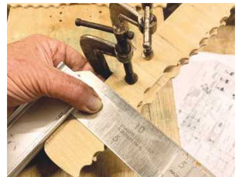
5 Clamp the wings and mark hole positions, using a square to ensure they're in line
