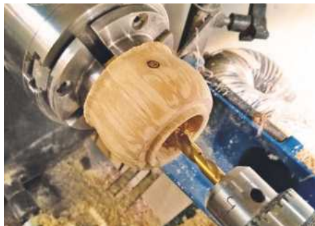
9 Use a 1.5in Forstner bit to bore a hole in the head section, while mounted on the lathe
