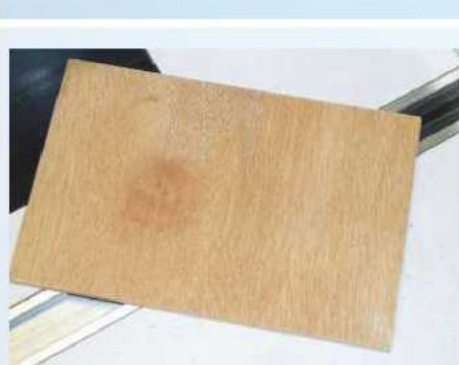
2 I used 5mm plywood offcuts for the base. Rout the sides and ends of the box to accommodate the plywood. This can be done using a rebate plane
