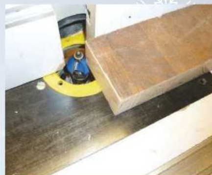
2 Chamfer all edges, except the base, using a router or sander/abrasives
