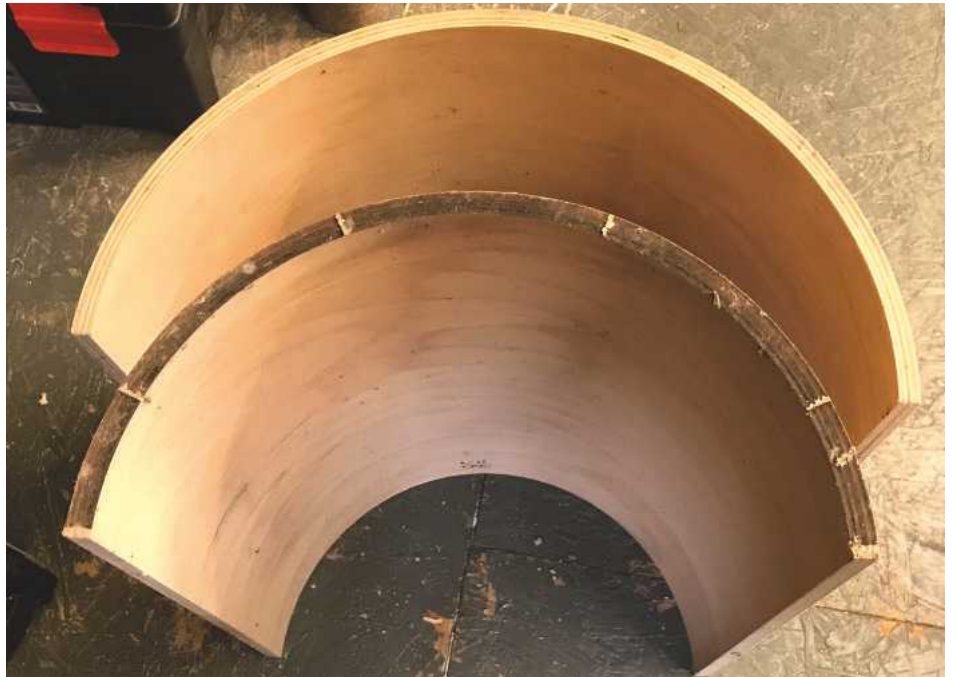
1 The starting point was a semicircle of birch ply measuring 600 × 600 × 300mm, with an 18mm thick radius
