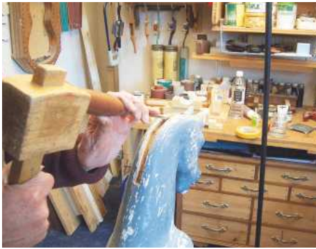
10 A 12mm paring chisel is used to hollow the channel to the correct depth
