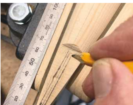
12 If you're using 4mm ply, mark two lines 4mm apart along this flat area and cut out using a fine saw
