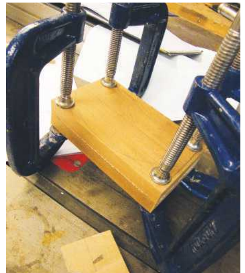
3 Softeners aren't required when clamping in the corners
