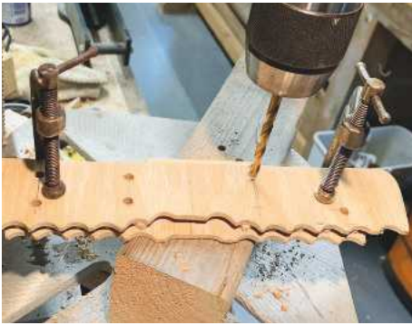
6 The holes need to be vertical to ensure the struts line up easily. Use a 5.5mm drill here
