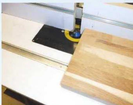
2 Rout or sand a chamfer on the top edge
