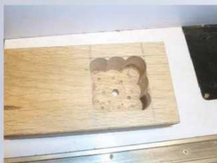
6 Use a Forstner bit to drill out a recess for the movement, then clean up using a chisel
