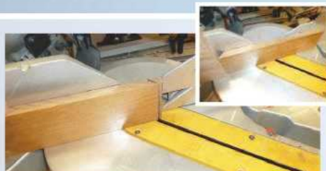
1 Decide on the length and width of your box. Set the mitre saw at 45° and cut the first mitre. Turn the wood over, place on mitre saw in the correct position, then clamp a square piece of wood to the saw so it's against the first mitre cut. Now cut the second mitre. With the wood clamped in place, set the saw to make the second box side so it's exactly the same length as the first; this is essential to ensure the box is square. Repeat for the box ends, resetting the clamped wood appropriately
