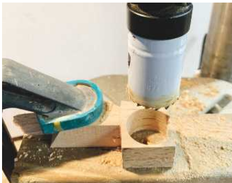
18 8mm dowel is required for the axle, and wheels can be cut from hardwood scrap; an 8.5mm hole ensures they turn freely
