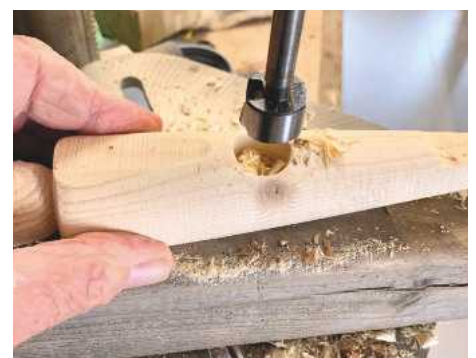
14 Cut a hole for the pilot, ideally using an 18mm Forstner bit mounted in a pillar drill
