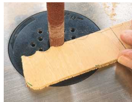
2 A bobbin sander is perfect for creating scalloped rear edges for the wing detail
