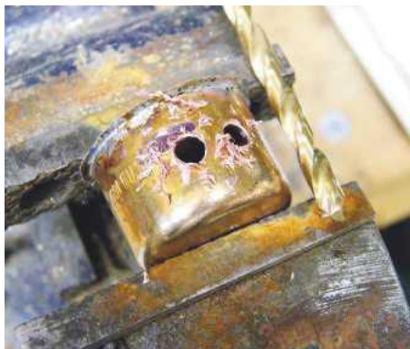
21 Ensure to use a slow drill speed when cutting metal
