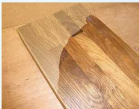
5 Finish with several coats of food-safe Danish oil using wire wool to apply
