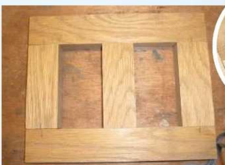
1 Cut uprights, cross rails and the rear support to size. If you have some form of jointer, join uprights to the cross rails. If not, drill, screw and plug – possibly using contrasting plugs for visual effect
