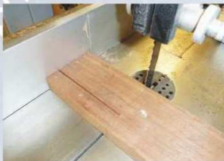
1 Cut a blank for the main body of the clock followed by contrasting wood for the base and head
