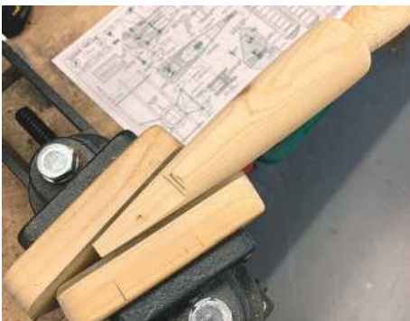
11 Shape the tail area almost to a point before filing another flat, this one for the triangular stabiliser
