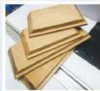
2 I used 5mm plywood offcuts for the base. Rout the sides and ends of the box to accommodate the plywood. This can be done using a rebate plane
