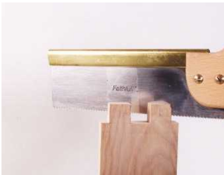
9 Cut slots for the wedges in the ends of the tenons. If preferred, these can be at 90° to the tenon face rather than 45°
