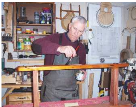
3 Polyurethane varnish provides a tough finish
