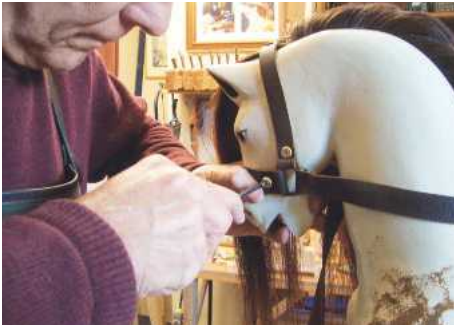
22 The bridle is screwed into place
