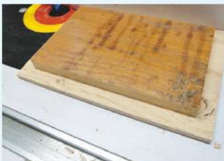
4 Carefully measure a piece of wood and cut to size for the top. As a rank amateur, I'm not up to precision fitting of hinges so plumped for a drop-in top. Measure the thickness of the sides and set a 3/4in straight router cutter and rout all round. You can also use a rebate plane if you wish
