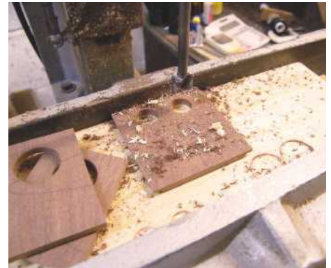
19 Drill suitable holes using a sacrificial piece of timber to prevent breakout
