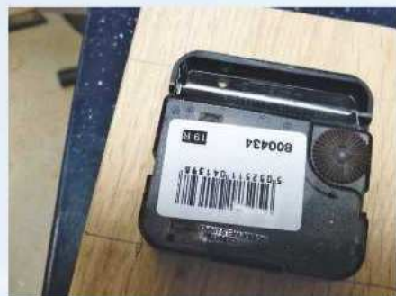
5 Turn over and insert movement shaft into the hole and mark around the movement
