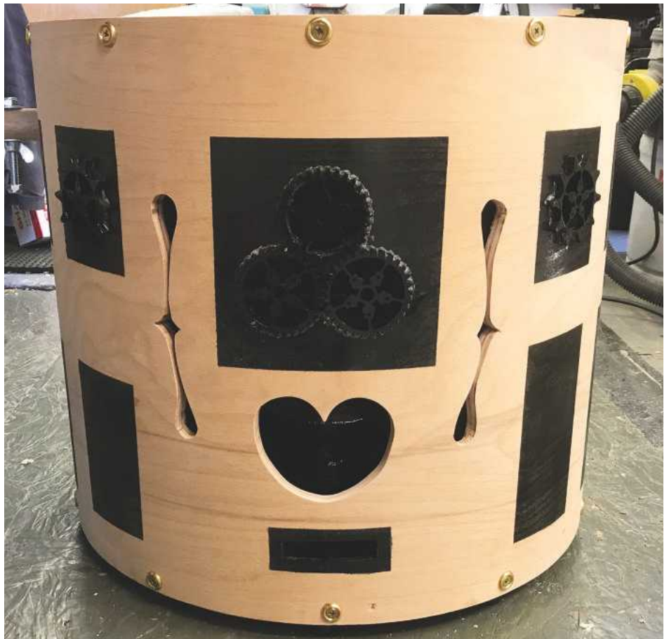
5 I screwed the top and bottom to the semicircle using five 50mm screws and screw cups. I decided to mask off a few squares and, using my previously made wine box guitar template, cut out two clefs
