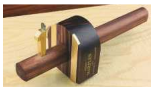
Cutting gauges are similar to marking gauges but have a small blade that's held in place with a brass wedge, instead of a pin
