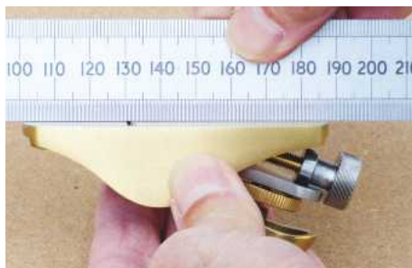
I checked the sole on this beautifully engineered plane with a steel rule, and it was almost perfect
