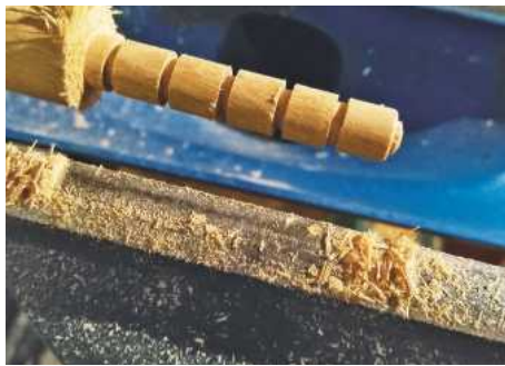
33 Turn the timber for the berries down to around 8mm diameter, dividing into sections using a parting tool, and mark out each of the barriers
