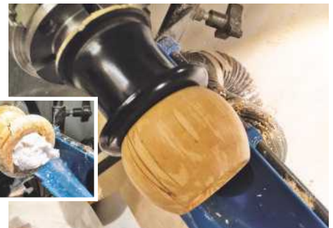
18 While mounted on the lathe, spray each hat with black lacquer, blocking up the hole with tissue paper
