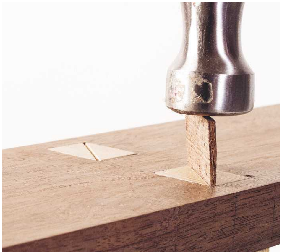
11 Assemble the joint and tap the wedges into place with a hammer. Once they're tight, trim off the tops and plane the ends of the tenons so they're flush with the surface ✂
