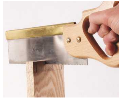
6 Saw out the tenon waste using a tenon saw. Make the vertical cuts first, ensuring to keep on the waste side of the marked lines
