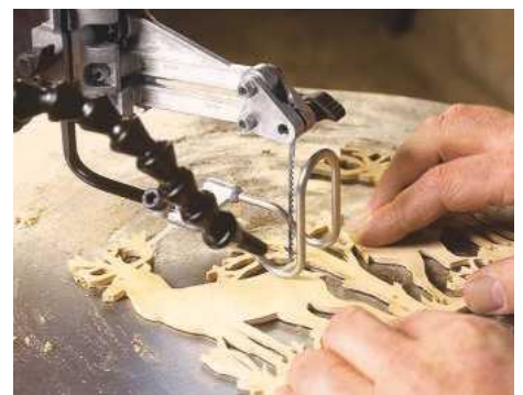
Many woodworkers use a scrollsaw for intricate pattern cutting
