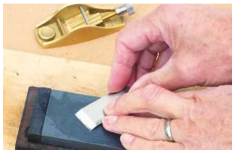
With a cutting angle of around 45°, honing the blade edge only takes a minute or so
