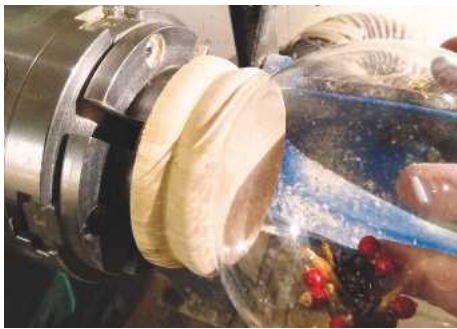
5 Remove material from the centre, occasionally stopping to test the fit of the bauble against the base
