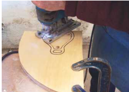
23 The stirrups' inside shape is cut out with a jigsaw
