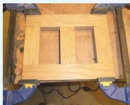
2 Assemble the frame with PVA glue and clamp overnight, ensuring the frame is square
