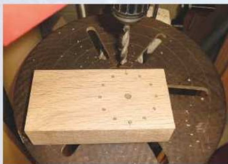
4 Centre punch for the centre hole and hour points. Drill a centre hole right through and to 5mm for the hour spots
