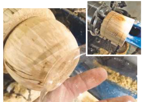
13 Use a spindle gouge to shape the timber, stopping the lathe so you can hold the glass bauble against it
