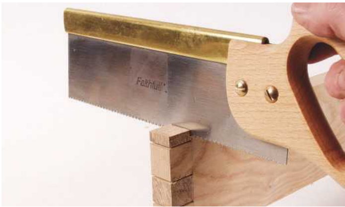
7 Next, carefully saw along the shoulder line at each side of the workpiece
