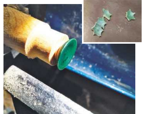
35 The leaves start off as discs, turned on the lathe; these are then coloured using a green Sharpie pen
