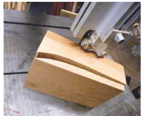
6 Cut to the waste side of the line
