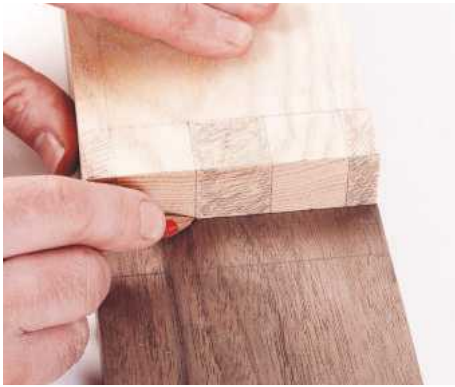
4 Transfer the marks from the tenon member onto both sides of the mortise member
