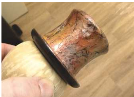
24 Before the paint dries, wipe off the excess from the areas you want to remain black – just the brims in this case
