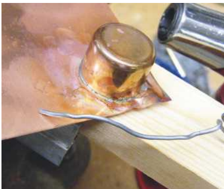
20 Solder the end cap onto a piece of copper sheet
