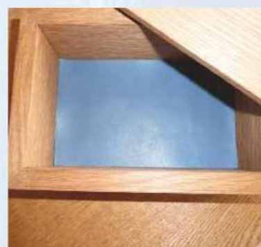
5 I had some leather left over from another project, so cut an oblong to drop into the box. You could also line the sides or paint the box interior if desired
