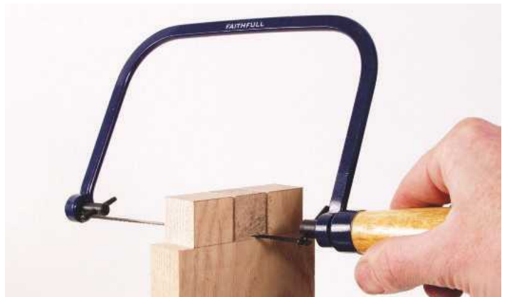
8 Use a coping saw to remove the section between the tenons. Keep on the waste side of the line, then trim down to it with a chisel
