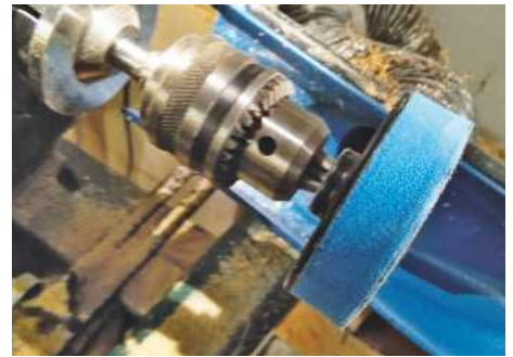
7 For sanding the base's underside, I use a sanding pad mounted in a chuck, which is attached to a No.1 Morse taper mandrel held in the headstock
