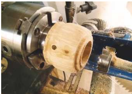
8 Mount the head blank on the lathe using the tenon formed earlier. Turn until roughly head-shaped, then create another tenon on the end
