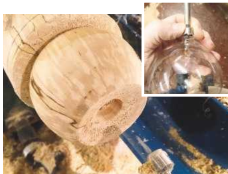
12 Remove the tenon, then use a small Forstner bit to drill a suitably sized hole to accept the neck of the bauble
