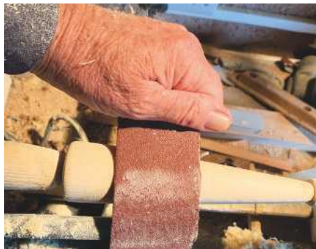
10 ... and sand from 50 x 50mm stock mounted on a small lathe
