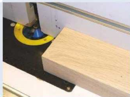
2 Chamfer the edges of your three clock components using a router or abrasives
