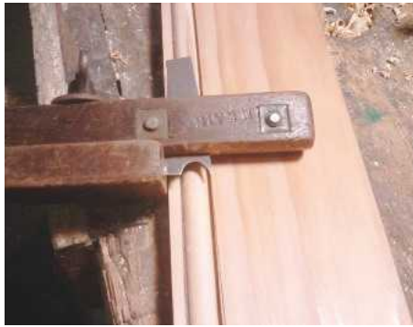
A scratch stock with \frac{1}{8} in radius beading cutter, and the resulting bead
