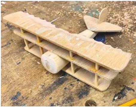
15 Line everything up so that it's parallel and square, and fix the middle wing in position with dabs of glue on the struts and fuselage
