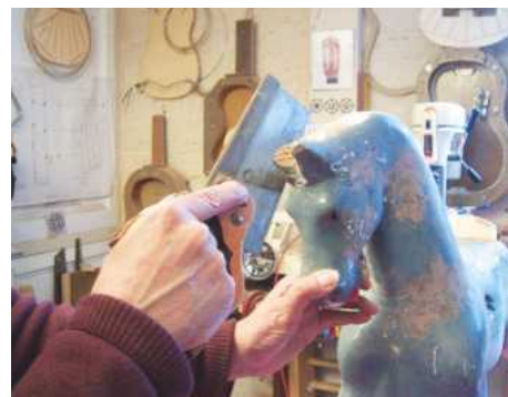
4 A dovetail saw is used to cut a flat part on the broken ear
