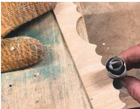
3 Twirl a sheet of 400 grit abrasive into a roll and begin to sand the detail
