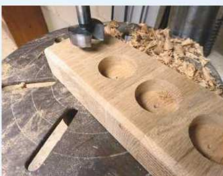
4 Drill to the depth of tealight you're using
