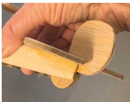
13 This slot will accept the fin and tail skid
