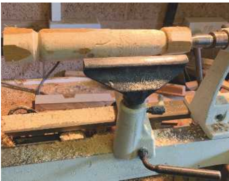
9 The fuselage is 40mm diameter at its widest and a simple job to turn...
