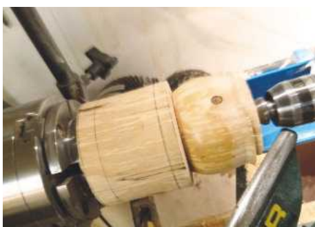
11 As the hat blank has a firm fit, use this as a friction chuck to hold the head; doing so will allow you to shape the underside
