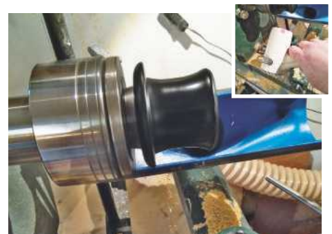
19 Once dry, turn each hat over, attached to the chuck in expansion mode, then remove the tenon before adding finish and lacquer
