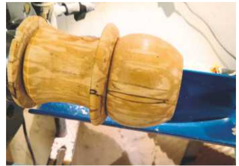
16 Once happy with the shape, sand and polish as before, using Yorkshire Grit, then attach the head so you can check the look and fit
