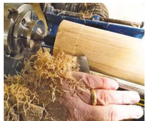
2 With bark removed, turn the log down to a cylinder, ready for marking up into three sections...
