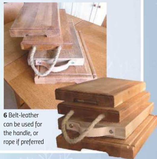
3 If you have a router, rout hand-holds in the lower ends
