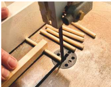
4 An easy setup for achieving this is a bench-top bandsaw and guide – ensure to use a push stick
