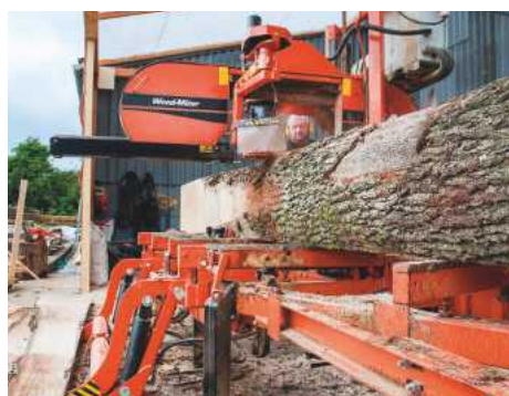
Sawing logs into finished lumber with a basic 'portable' sawmill
