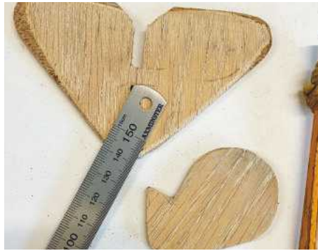
7 The triangular horizontal stabiliser and a small vertical fin and skid are both made from ply
