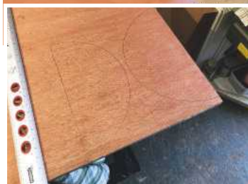
2 Next, I marked out two semicircles on a sheet of 18mm ply, for the top and bottom of the instrument
