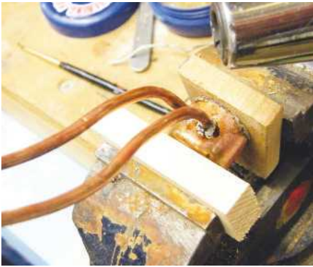
23 The scrap wood acts as an insulator/heat shield on the vice
