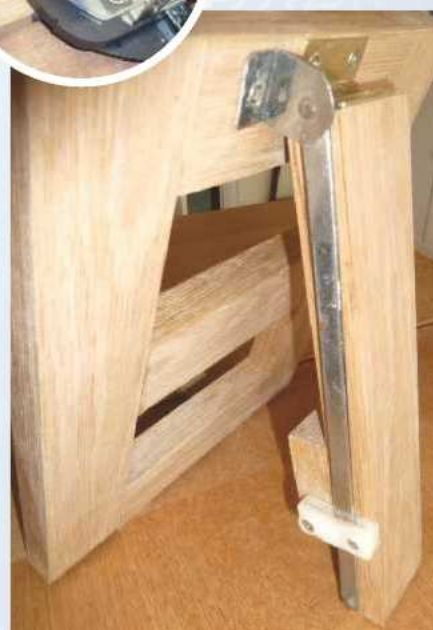
4 Add rear support with a hinge and stay on the side of the support. Finally, sand and finish with matt varnish
