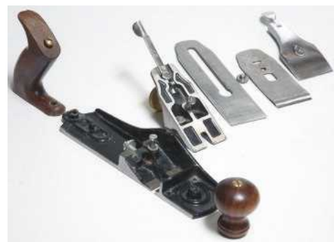
3 Dismantled – left to right: rear handle, body and front knob. Behind these are the frog, cutting iron, cap iron and lever cap
