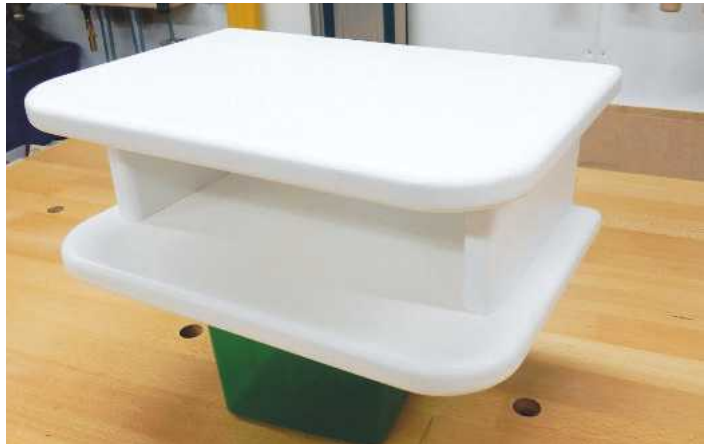
24 Just when I thought I'd finished, along came my daughter and said: "Oh, they're nice – can I have one but in white?" There's no point in using good hardwood if a painted finish is to be applied, so I used some moisture-resistant MDF I had left-over from another project. This type of MDF is considered slightly denser than standard and doesn't go quite as fibrous on the edges. The overall dimensions are 300 × 200 × 110mm
