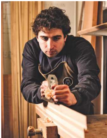
Planing the laminated core to size
