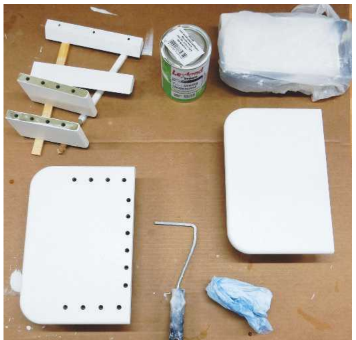
29 After sanding, using a foam roller, I applied a coat of clear MDF sealer followed by two coats of water-based undercoat and two coats of satin top coat. This gives a slightly stippled finish, which helps to hide any small defects in the surface ✕
