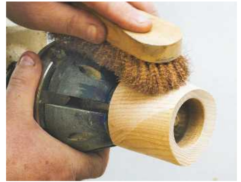
17 Start by picking out some of the soft grain with a bronze brush
