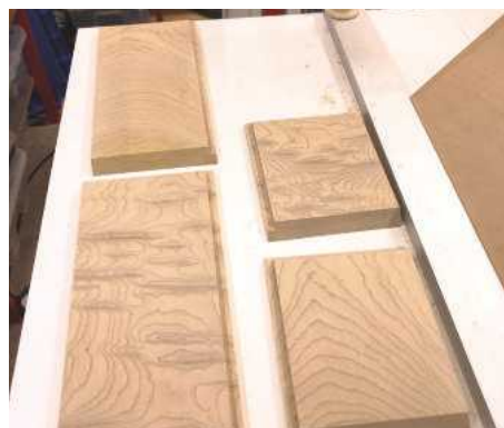
3 Box sides complete with rebate and mitre, ready for assembly
