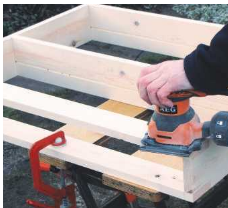
20 Fill nail holes and any knots before sanding all surfaces with 150 grit abrasive
