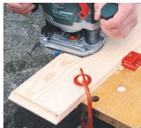
21 Rout a profile around the overhanging top. A 10mm core bit creates an elegant coving
