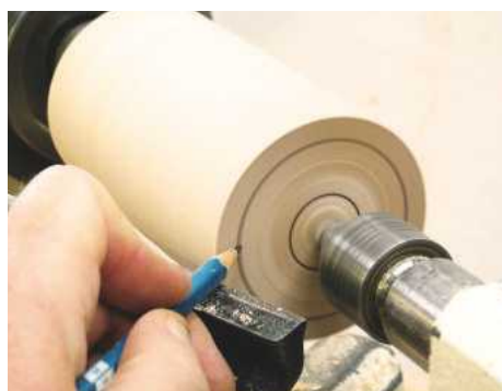
1 Turn each blank to a cylinder and draw two concentric circles on each end
