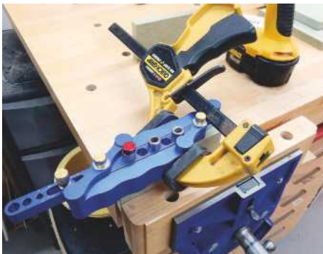
25 This time, instead of biscuit jointing, I tried out my new dowel jig. This jig is only designed to work on the edge of a board – it's self-centring and comes supplied with sets of 6, 8 and 10mm bushes. It's supposed to be hand-held but I prefer to clamp it in place. I've only ever seen these jigs online and I bought mine via Amazon, which at the time, was cheaper than anywhere else I could find. If I had to score it out of five, I'd give it a four – it's good but not perfect and is limited in application
