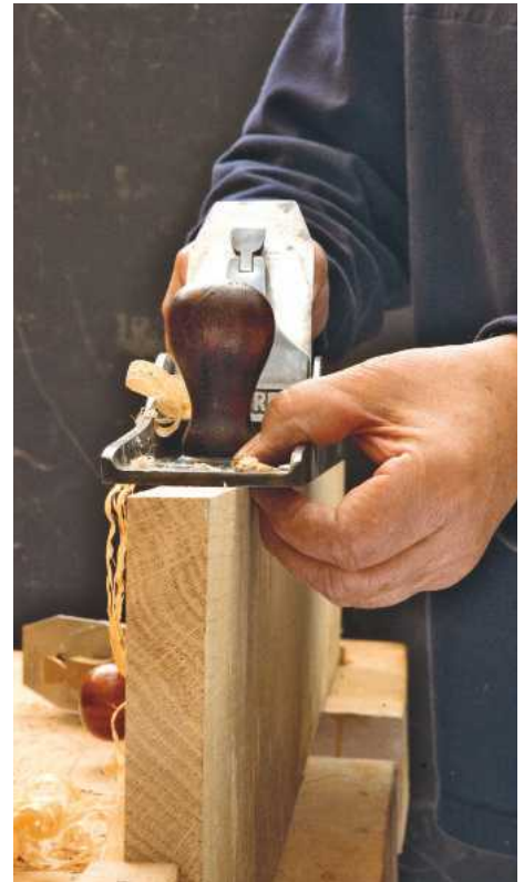
13 The board is clamped with one edge up and the plane run along it with the grain. Fingers, under the plane's sole, guide and keep it centred on the edge
