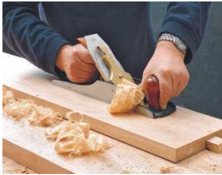
12 The first step is establishing one flat face. This will be a reference surface for the edges and other face
