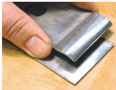
8 The cap iron, or 'chipbreaker', sits tightly against the cutting iron
