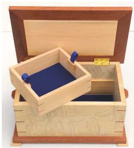
14 Neat little cedar blocks hold the ribbon handle loops in place
