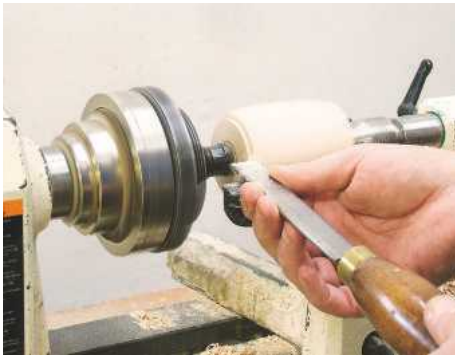
15 Mount the blank on its true centres and turn a chucking spigot on the base
