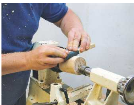
13 Next, stop the lathe and sand the surface with the grain, keeping the edges crisp
