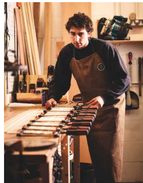
Clamping the core together
