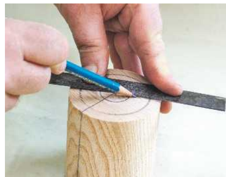
8 Draw radial lines from these marks to the centre point at each end of each blank
