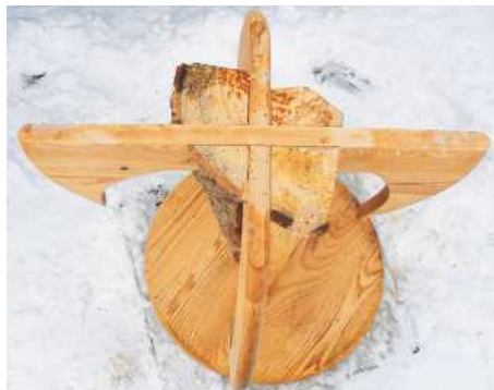
6 The interlocking feet are housed in the base of the ash column
