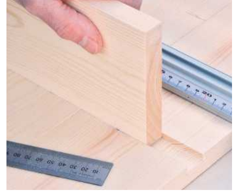
3 Check that the shelf ends fit snugly into their housings, and adjust the width of the routed trenches if necessary
