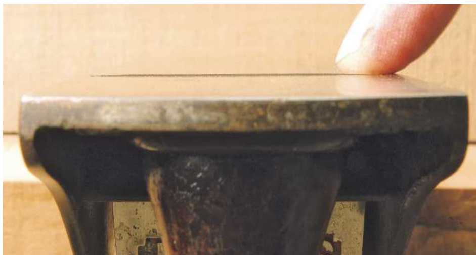
9 With the plane held upside down it's possible to see the cutting edge protruding through the mouth, level across most of its width, sloping down slightly at each side
