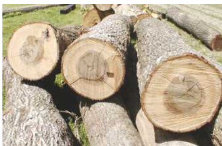
Ring shake visible in some hickory logs
