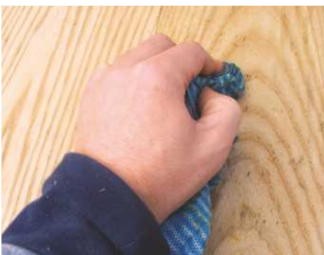
7 After sanding, the whole table was finished with linseed oil, which raised the grain of the ash...
