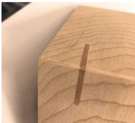
8 Mahogany keys inserted, cut and sanded smooth. Take your time with this step
