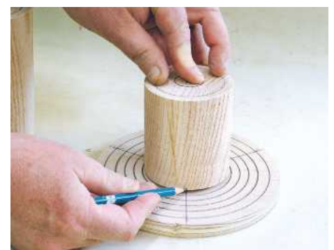
6 Centre your turned blank on the jig and transfer the radial lines to it
