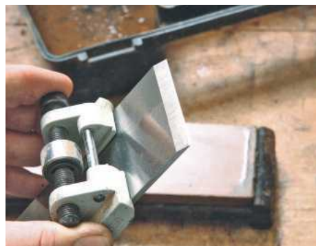
5 The tip of the cutting iron has a fine bevelled edge, which is typically ground at 30°
