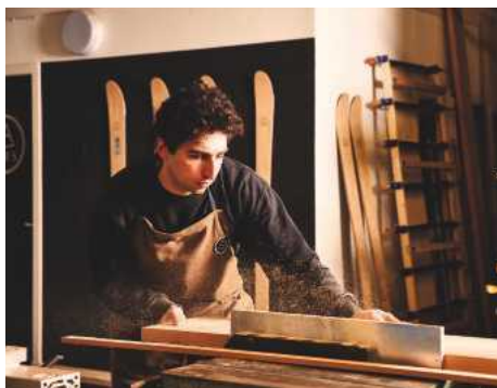
Ripping beech to make the laminated cores
