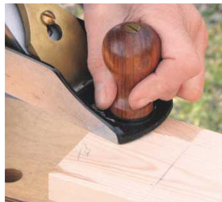
15 Plane the end-grain flush, working in towards the carcass to prevent timber splitting
