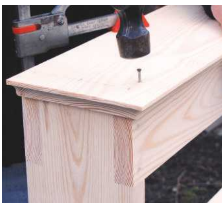
22 Cramp the top to the carcass and nail down into the front and rear valances
