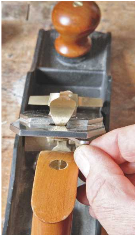
11 The lateral adjuster moves from side to side in order to level the depth of cut
