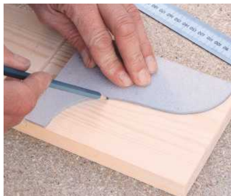
5 Carefully mark and cut out a card template, then draw around its outline on to the side components
