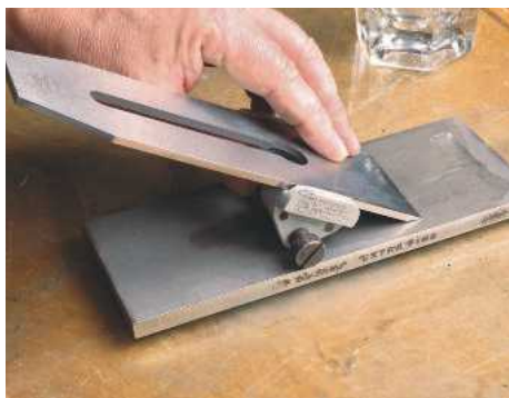
4 Sharpening the plane's cutting iron using a honing guide and diamond bench stone
