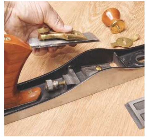
19 A block plane with its cutting iron mounted bevel-up has a simpler design than the normal bench plane
