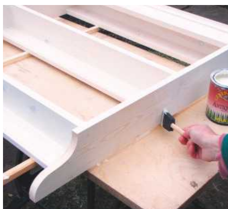
23 Sand the arrises and you're then ready for finishing; if painting, I find a foam pad works best when using acrylic paints
