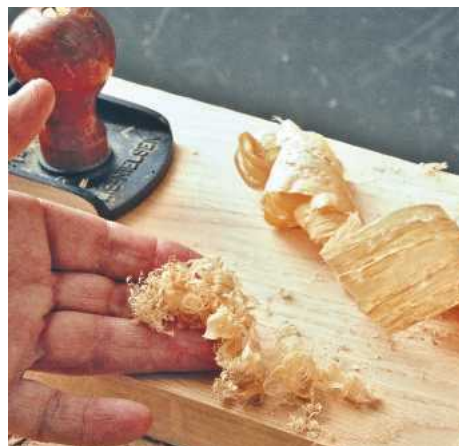
10 If the cutter is set too shallow, the fine wispy shavings drop to pieces – as shown left – and if it's too deep, the shavings will tear out and leave a rough surface – as shown right
