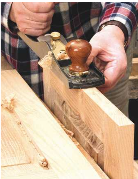
20 The low-angle jack plane is ideal for straightening edges of frames, such as when fitting cabinet doors
