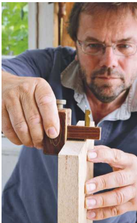
15 With one face and edges true, a marking gauge draws thickness lines around the edges
