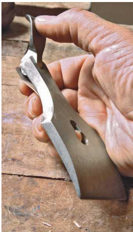
7 The lever cap clamps the cutting assembly in place against the frog
