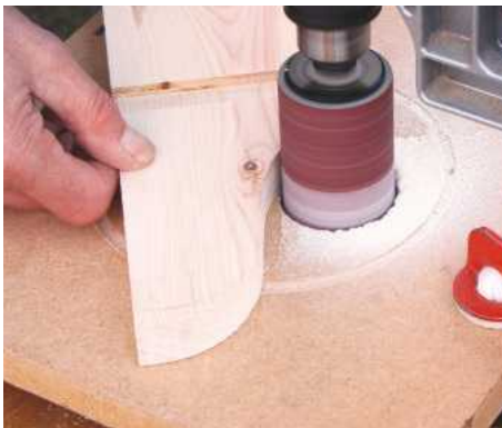
7 Clean up the sawn curves; if you have a drillstand, a sanding drum makes light work of this job
