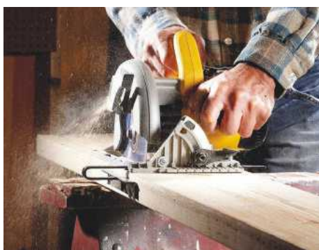
Ripping wood using a circular saw
