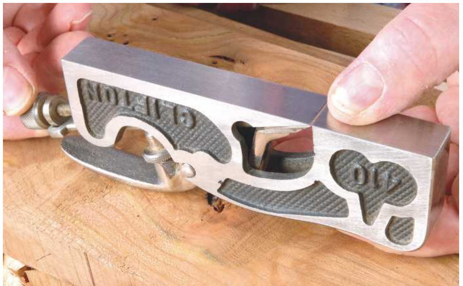
21 There are many small planes for specialised jobs and one of the most useful and versatile is the shoulder plane
