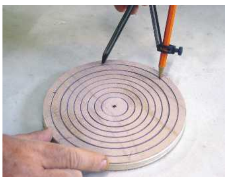
4 Set the compasses to the outer circle's radius and step round the circumference six times
