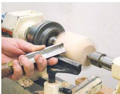
10 Mount the blank using centre '1' at the headstock and '2' at the tailstock end, then turn the first side
