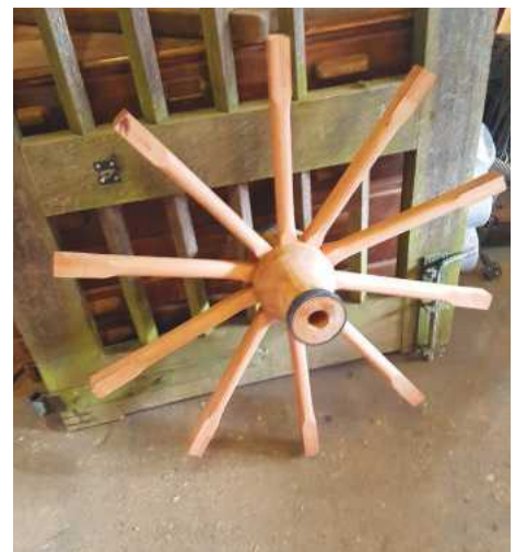
Tenons with tongues visible at the end of the spoke
