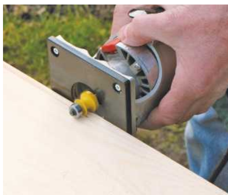
17 Rout a beading along the lower edges of stretchers with a bearing-guided bit
