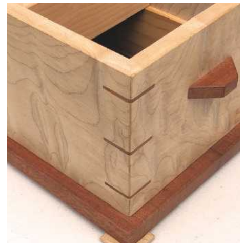
15 25mm square sycamore feet were added later; these improve the look of the box and the felt placed underneath these prevents scratching
