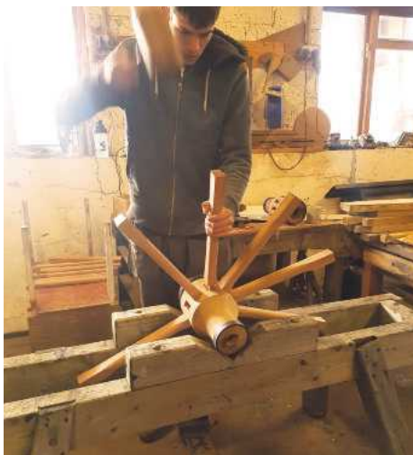
The spokes are driven into the hub using a hammer
