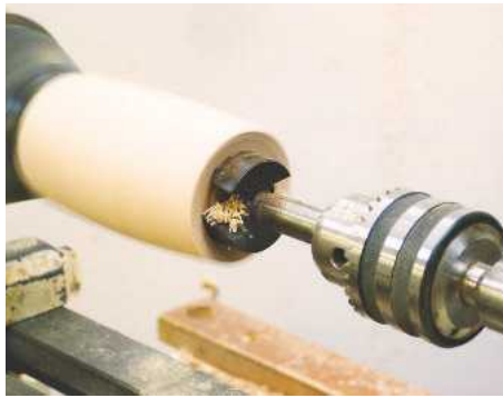
16 Use a sawtooth bit in the tailstock to drill the recess for the tealight
