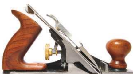
2 An ordinary bench plane, or 'Bailey plane', with one side cut away
