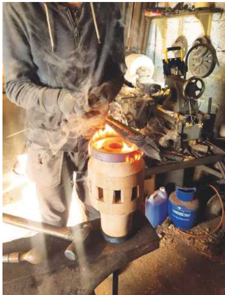
Applying the hub rings
