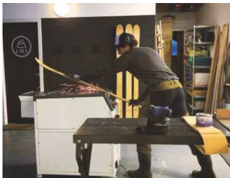
Flattening the base and sharpening steel edges
