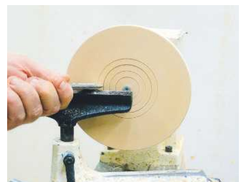
3 Turn a plywood or MDF disc and cut a number of concentric circles into its face
