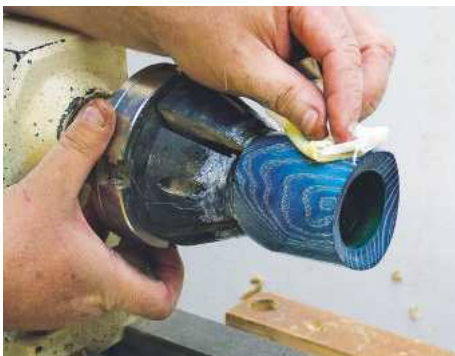
20 Make sure you've filled all the grain, then remove any excess with Danish oil
