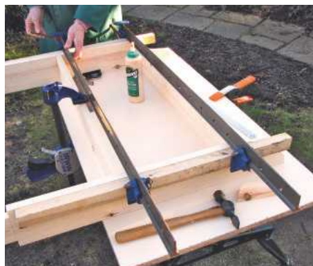
11 Cramp the frame together and check for square; measuring across diagonals is the most reliable way – a square frame will give equal diagonal distances
