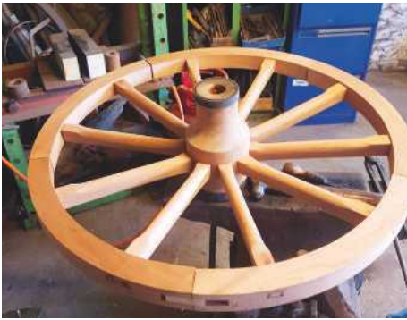
Five felloes have jointed wooden dowels
