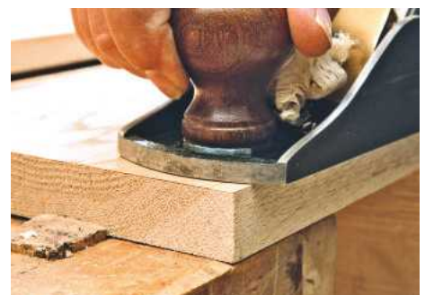
16 The second face is planed down to the line leaving the board a uniform thickness all over
