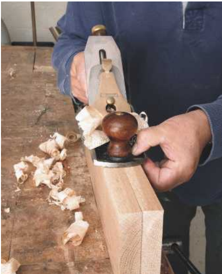
17 Edges to be joined together are planed as a pair. Any slight inaccuracies in the angles will cancel out when pressed together
