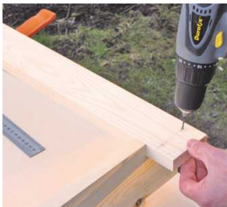
13 Cut the front valance overlength and nail to the sides; pre-drill the holes to stop splitting
