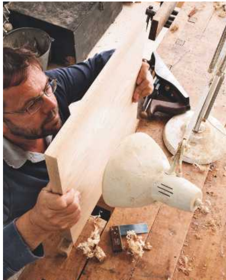
18 Boards are pressed edge-to-edge as a trial fit with a lamp placed behind to highlight any gaps between them
