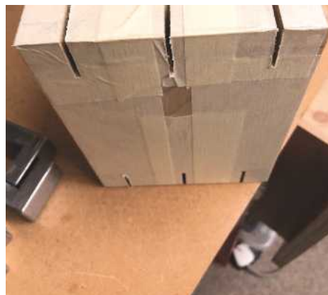
7 The tape protects the faces of the box while the slots are machined
