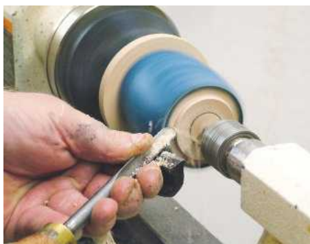
22 Turn away the spigot and adjust the heights of each tealight to keep the 1:1.6 ratio
