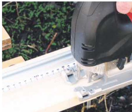
8 Saw notches at the upper end of each side for front and rear valances
