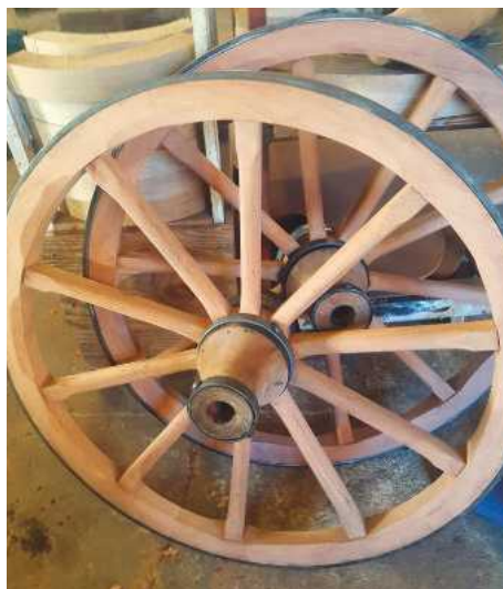
Hub rings will be positioned either side of the spokes
