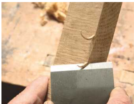
6 Testing the sharpness of the edge by slicing through oak end-grain
