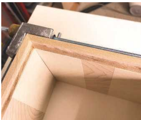
5 It's worth protecting the finished insides as any glue will be difficult to clean up later
