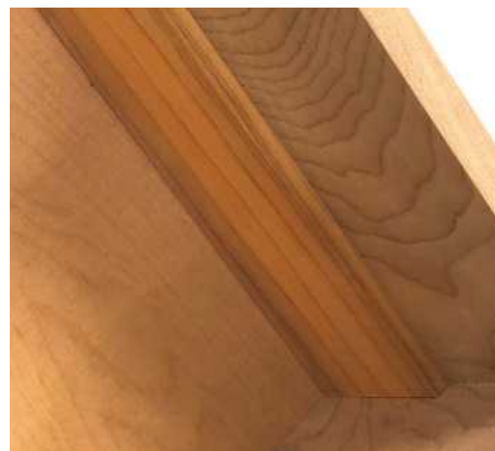
9 Cedar drawer runner added to the bottom of the long side
