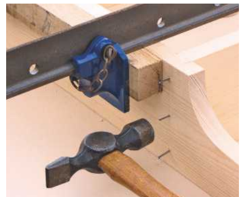
12 Nail the sides and shelves together, punching the heads below the surface
