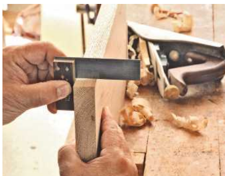
14 Using a try square to check that the edges are at right angles to the flat face
