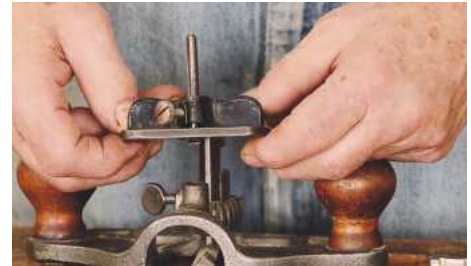
Antique woodworking router plane in use
