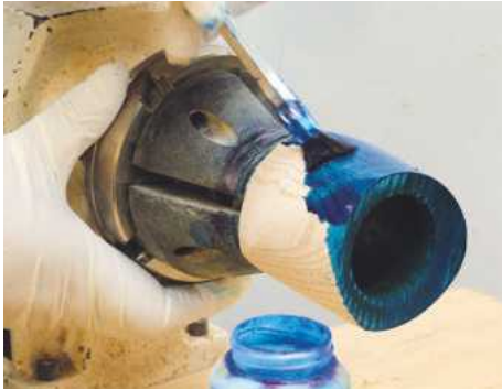
18 I used a spirit-based stain, then sealed the surface with sanding sealer
