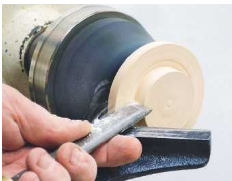
21 Mount some scrap wood in the chuck and turn a spigot to fit the tealight recess
