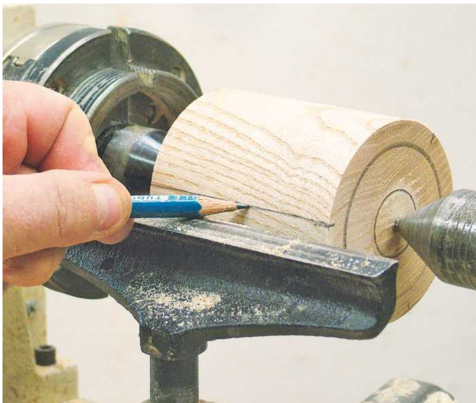
7 Use the toolrest to transfer these marks to the other end of the blank
