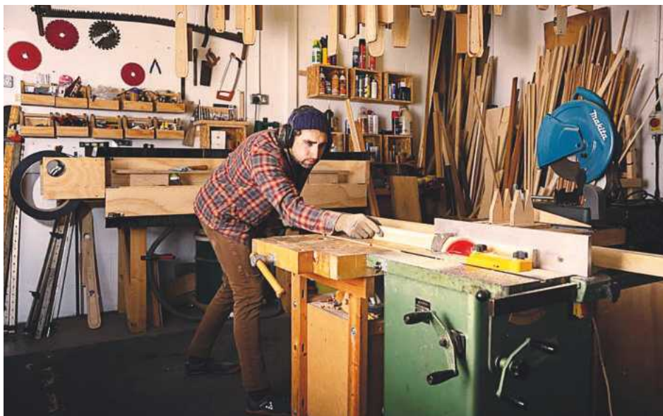
Dimensioning pieces of beech and poplar for a batch of ski cores
