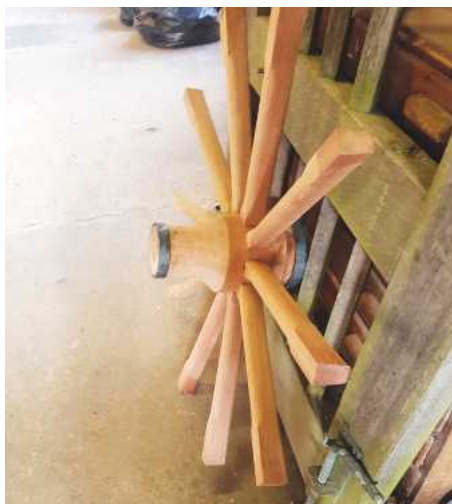
All 10 spokes are driven in with tenons, ready to go into the felloes
