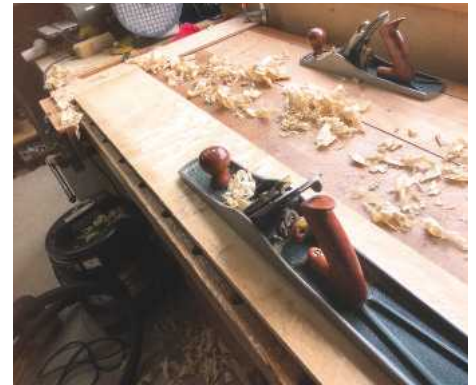
1 Preparation of the sycamore using a finely-set bench plane
