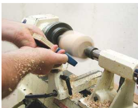
12 Wrap the abrasive round a wooden block and sand each side with the lathe rotating
