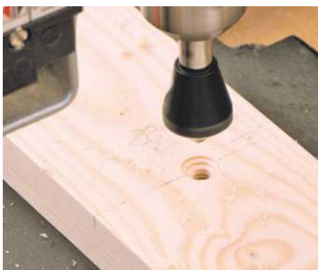
16 Drill and countersink holes in the rear valance for screw fixing to the wall
