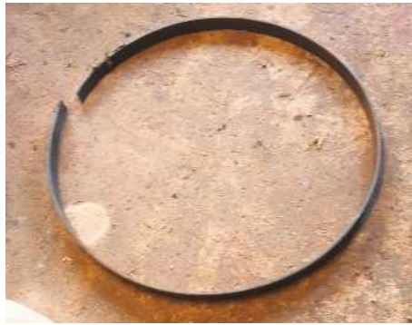
Tyre ready to be butt welded
