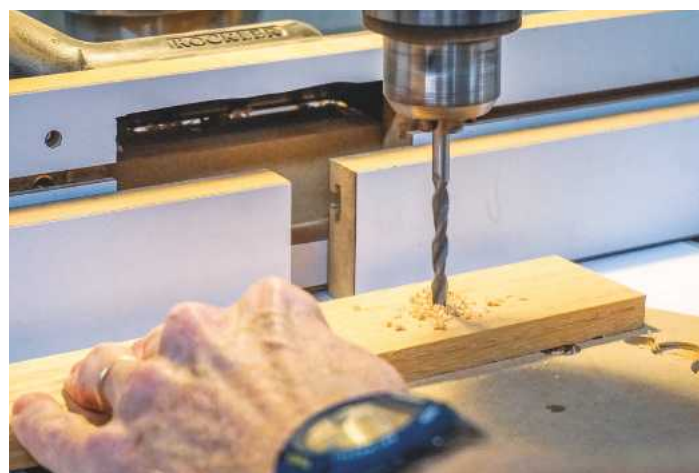
3 Preparing the guide with a 6mm hole
