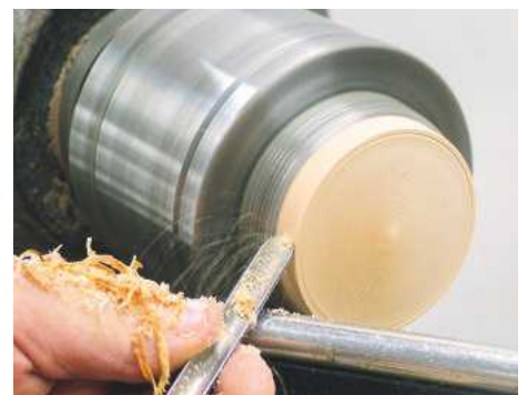
14 Reduce the plug to the correct diameter and cut a small chamfer
