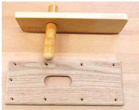
8 The latch was then waxed and the handle given three coats of exterior varnish. The cover for the inside was a piece of thin oak from my odds and ends bin
