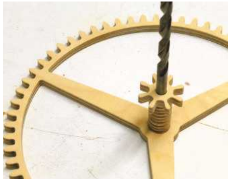
5 Align the gear, the small pinion and spacer on a drill bit...
