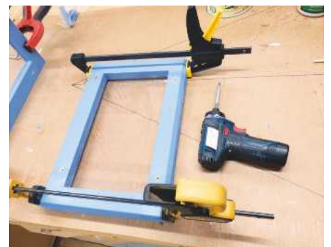
11 Two clamps were used to keep the two frame halves aligned while screws were inserted into recessed holes, which would hold them together
