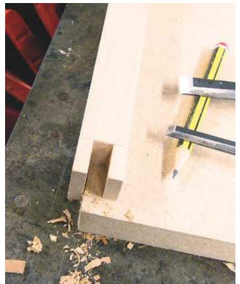
16 Use a sharp chisel to square the end of the opening
