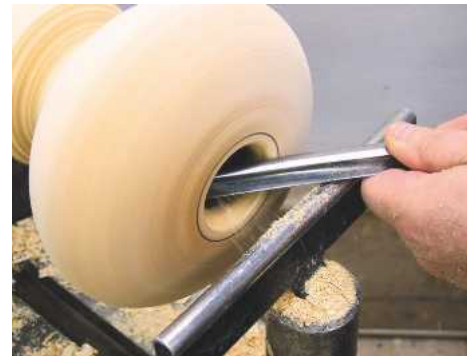
9 Use a bigger gouge to cut deeper into the cavity...
