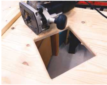
6 A diamond-shaped opening was carefully cut out using a jigsaw, the edges sanded flat, then the inside rounded over using a router
