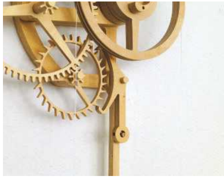
17 ...and adjusted to bear against the peg on the pendulum
