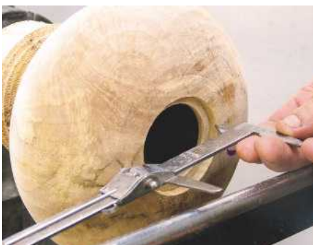
12 ... and measure its diameter
