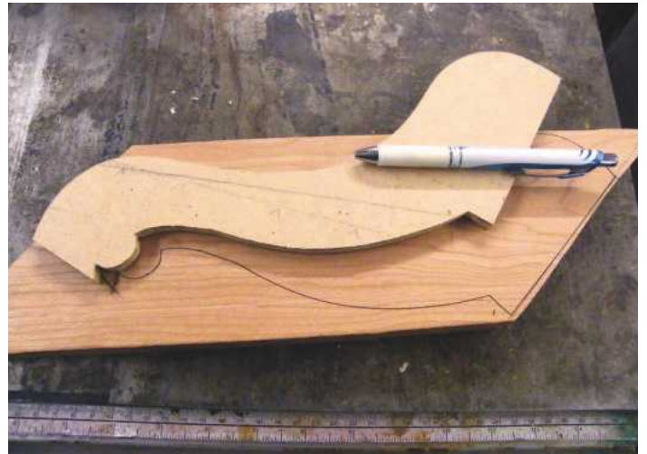
1 Make an MDF or card template detailing the outline of one foot
