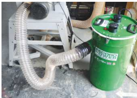
Connected to the outlet of a 14in Record Power bandsaw, the CamVac sucked effectively with just one motor activated
