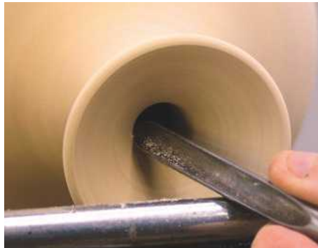
19 ... and carefully shape the inside neck, breaking through to the cavity
