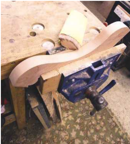
3 Sand the sawn faces to remove any saw marks
