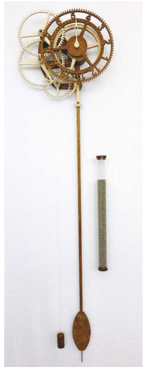
20 The drive and counterweights complete the clock assembly
