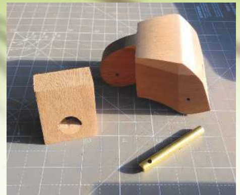
2 Head blank and body. The head has been drilled and plugged with half a dowel, the body cleaned up and drilled with 3mm holes for the connecting pins
