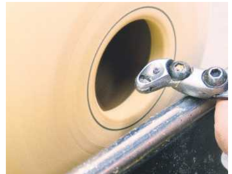
10 ... and a cranked or articulated tool to remove wood next to the opening
