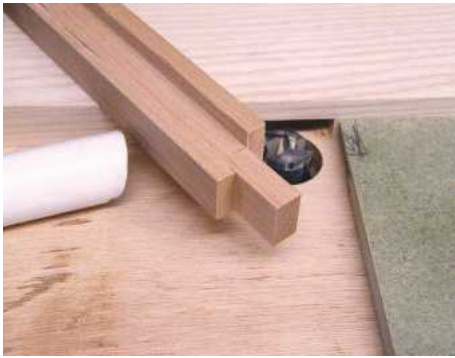
20 Adjust the depth of cut a little at a time...
