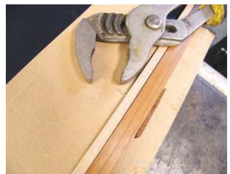
25 Using a pair of slip joint pliers or similar, the beading can be effectively held in place
