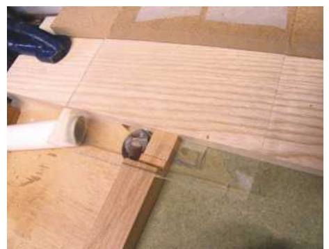
19 Position the MDF offcut so that it's perpendicular to the fence
