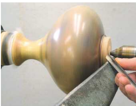
28 Reverse the piece onto a dolly and turn away the spigot
