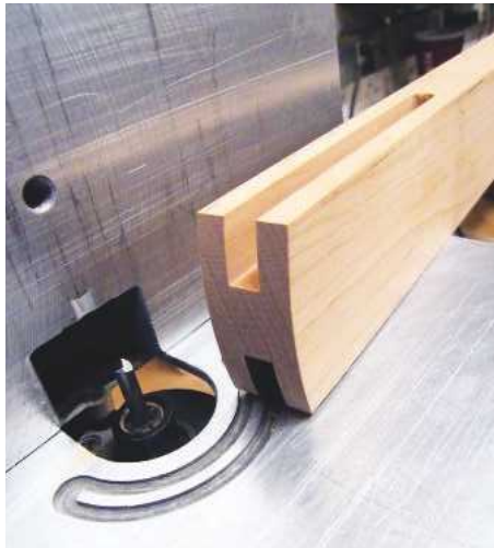
4 Cut the grooves using a router table
