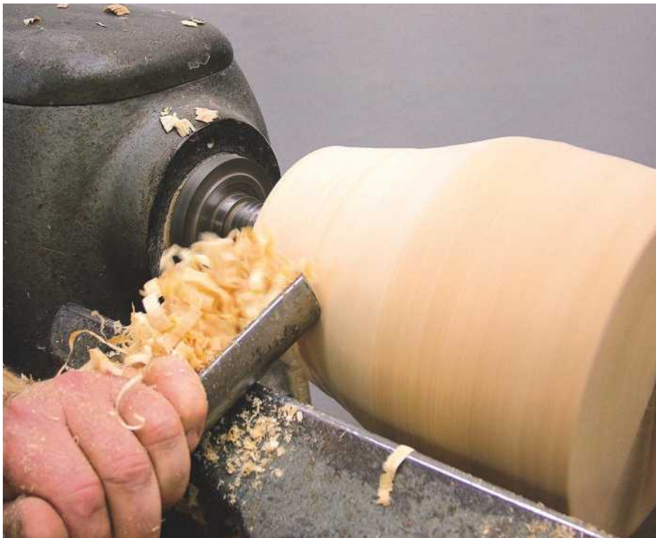
1 Turn your blank to a cylinder and start shaping
