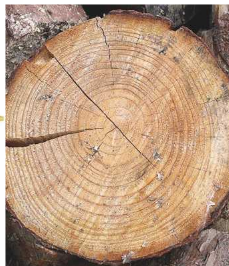
Radial shake in a cross-section of timber
