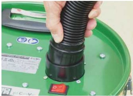
Fitting an additional hose cuts noise levels, but a pair of acoustic outlets allows for maximum benefit
