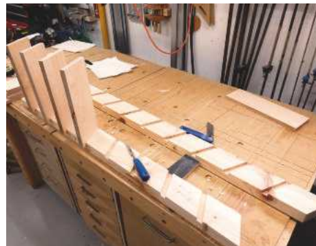
14 I've never made stairs before, but found this easier than anticipated. Using 4x2in scant, the required angle for the side rails – 65° from horizontal – was largely dictated by the amount of space available
