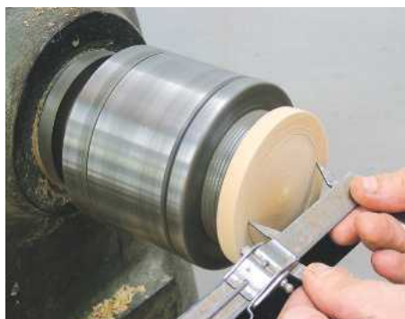
13 Transfer the diameter of the opening to the plug
