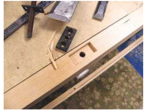
22 As before, use a sharp chisel to remove the waste
