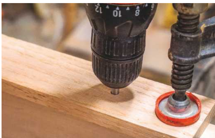
4 Drilling a cylinder around the screw
