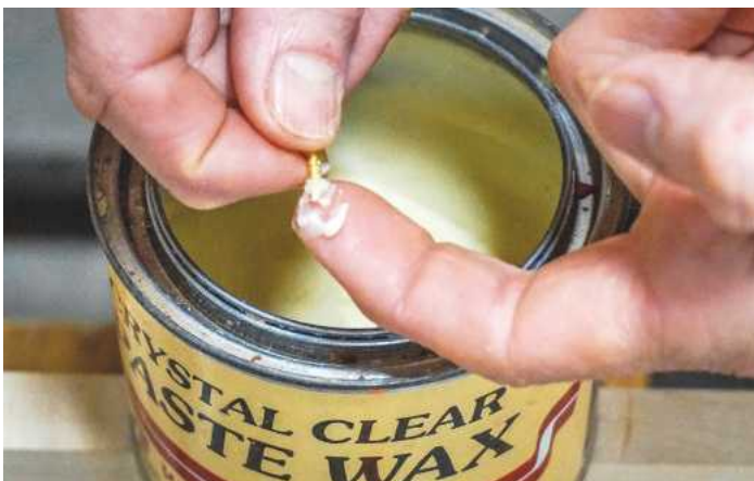
11 Applying a little wax to the screw threads
