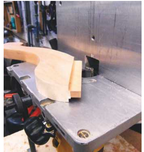
5 Note masking tape in place to prevent breakout
