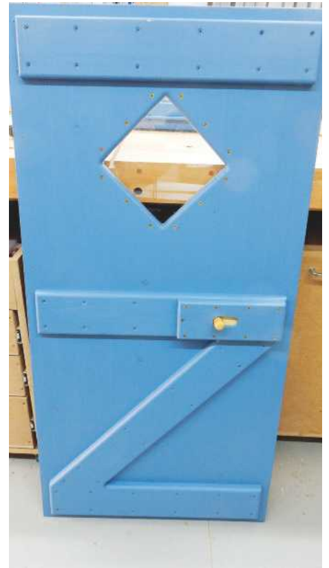
9 The completed door having received two coats of paint. The window panel sits in rebates in the external trim, with glazing silicon used to seal it in place
