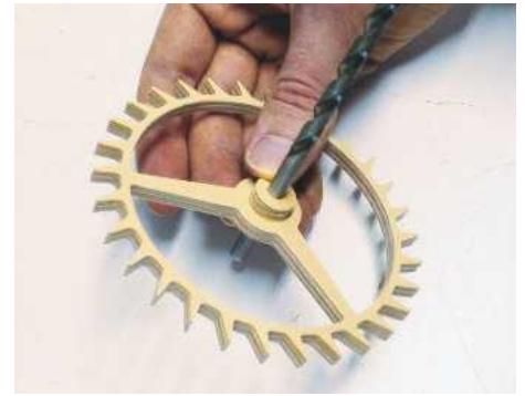
3 The escape wheel and spacer can be centred on a twist drill bit...
