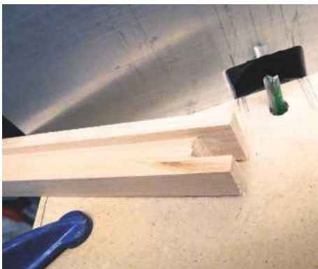
15 Pencil marks on the false table assist with positioning the wood
