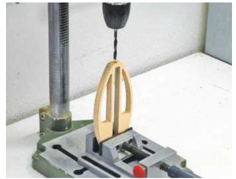
10 The end of the pendulum bob is drilled to take the adjuster rod
