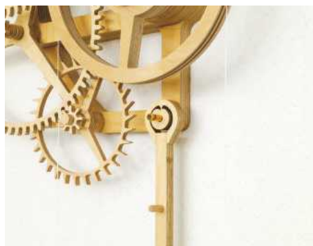
14 The finished pendulum can now be suspended on its pivot
