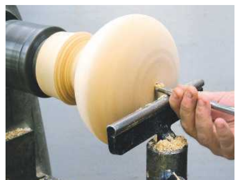
7 Start boring the hole using a spindle gouge
