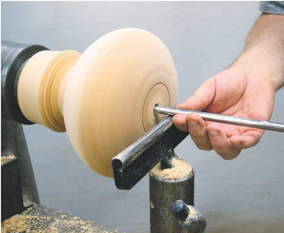
8 Hollow the vase, starting in the hole and swinging the handle away from you, making the cut on the left wing of the gouge
