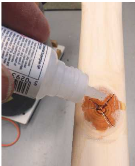
17 I discovered a couple of knots in the side rails, so these were soaked with thin CA adhesive to stabilise them
