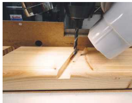
16 The holes in the side rails were drilled out bigger, providing clearance for the screws, then countersunk
