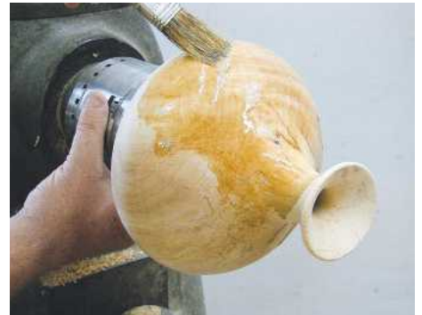
20 Sand and finish with two coats of sanding sealer
