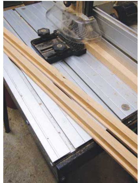
14 Note use of pressure pad on the router table
