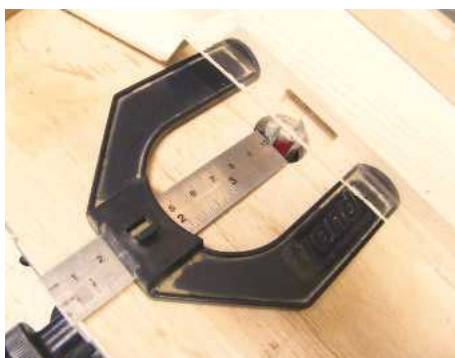
18 Clamp a false fence to the router table
