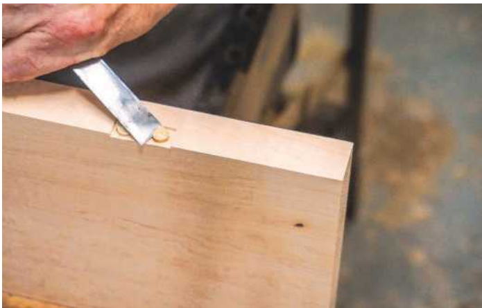
9 Chiselling the dowel flush
