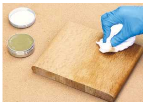
After rubbing on three or four coats of wax with a lint-free cloth, a lovely silky sheen became evident
