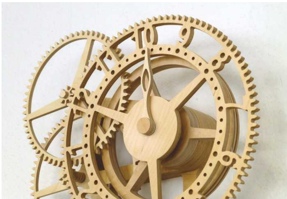
19 The hour wheel can now be set in position – note the fixed hour hand
