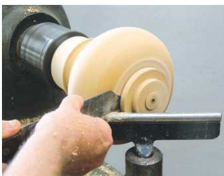
5 Use a narrow parting tool to cut off the spigot...
