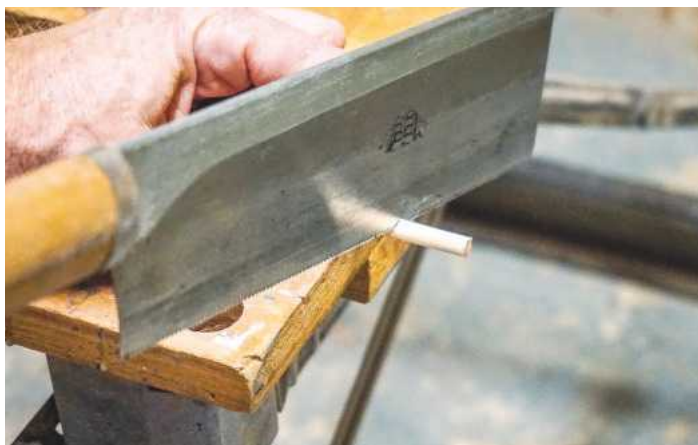
6 Cutting dowels to plug the holes
