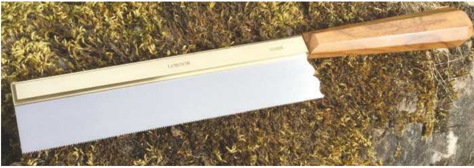
Archer Saw – 7½in fine gent's saw with tapered semi-symmetrical octagonal handle in flamed beech. Rear of the blade features a unique Cupid's bow, plus a skilfully crafted complementary Cupid's arrow in the brass back
