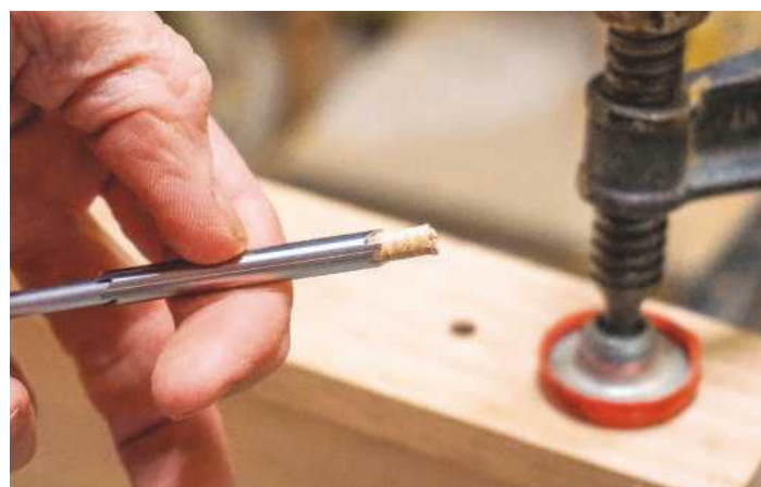
5 Removing a cylinder of wood around the embedded screw using the extractor
