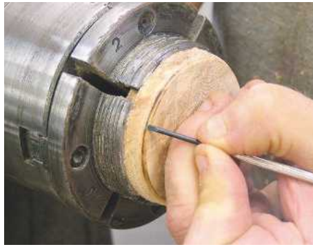
16 ... which should leave a slight burnish mark
