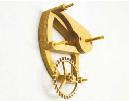
4 ... and fitted to the lowest frame arbor along with a pinion
