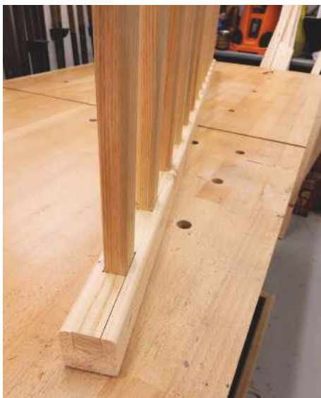
18 Using multiple passes on the table saw, I created a rail for the upper floor. I cut a wide slot along two lengths of 2x2in scant, ensuring it was wide enough to accept some lengths of recycled ash batten I'd been given
