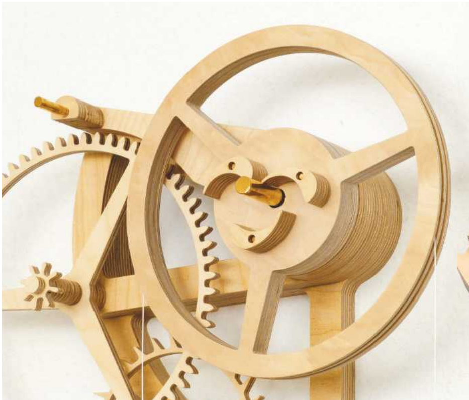
9 The ratchets will engage with the cog on the back of the hour wheel
