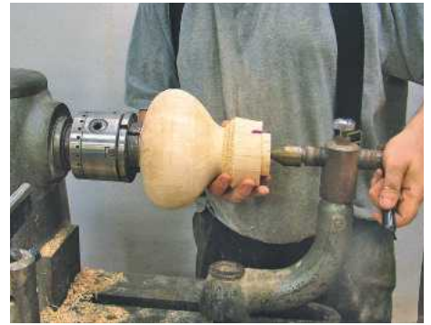
17 Glue the plug in place and use the tailstock as a clamp
