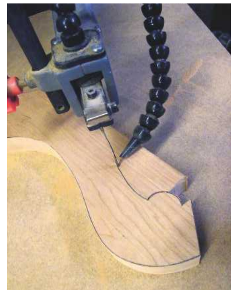
2 Cut the shape out using a scrollsaw or similar
