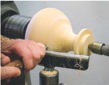
18 Carry out final shaping of the outside using a spindle gouge....
