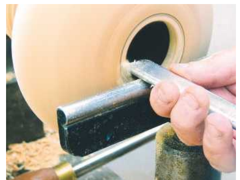
11 Cut a parallel-sided stepped recess at the vase's opening...
