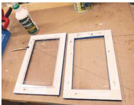
10 For the side windows, I made each half from two simple frames, held together with glue and a single pocket-hole screw at each butt joint
