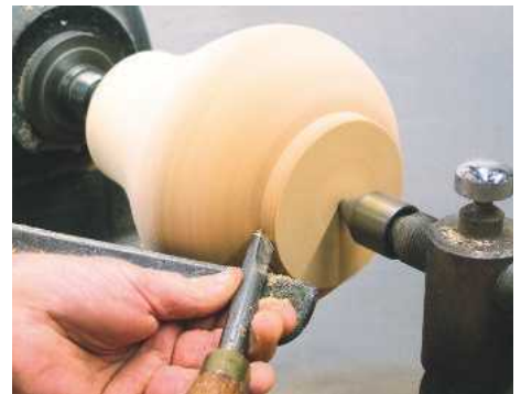
2 Refine the shape using a spindle gouge
