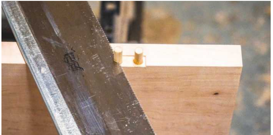
8 Trimming dowels with a saw
