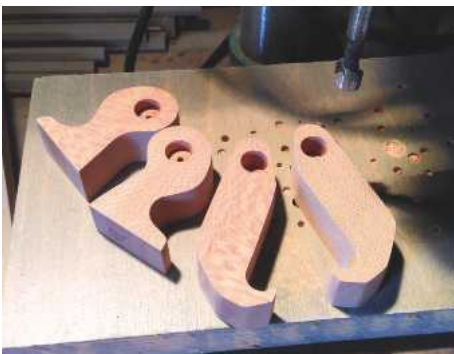
4 The arms and legs have a 15mm recess drilled part-way, which houses the Starlock washers
