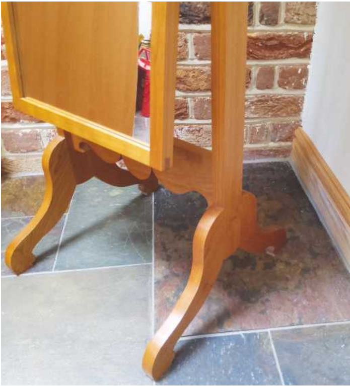
1 Make an MDF or card template detailing the outline of one foot
