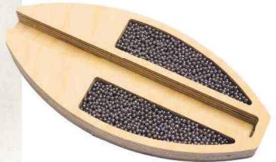
11 The hollow central section of the bob is filled with lead shot...
