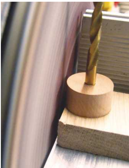
23 Using a simple jig, small diameters can be cut with care
