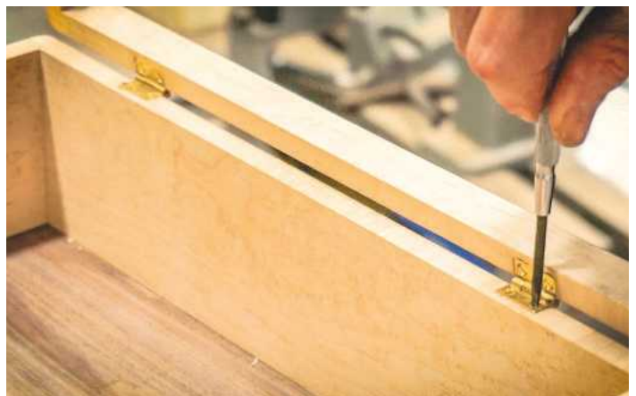
12 Using the correct size screwdriver to tighten the screws
