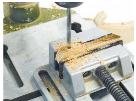
15 The anchor is drilled to accept the two small adjusting grub screws
