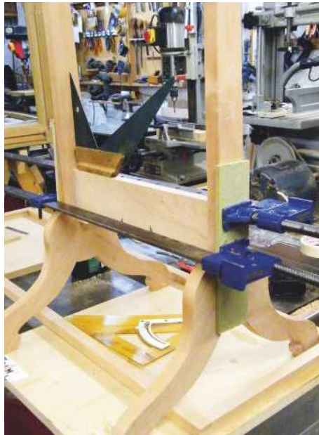
13 The base can now be glued together
