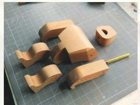
3 Ready for test assembly; note 6mm brass tube (drilled), which secures the head to the body
