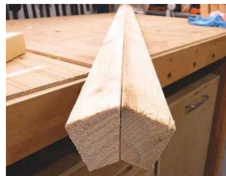
4 To create the substantial ridge piece required, I set my table saw at 25° and ripped the edges from two lengths of 2×2in scant
