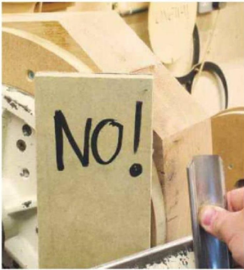
20 Never use the spindle roughing gouge on grain orientation like this; it'll grab the end-grain as it revolves, causing a major accident, and even leading to tool breakage in some cases
