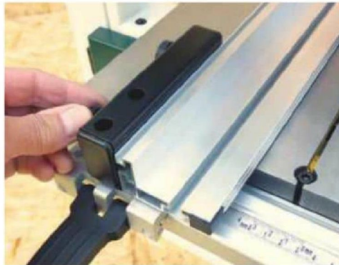
Depending on material thickness, you can mount the fence horizontally or vertically, with appropriate T-slots accepting the T-bar
