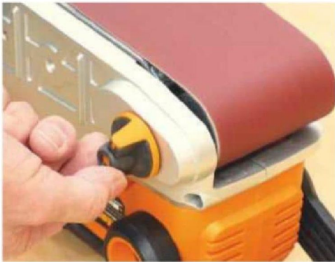
A knob at the end of the front roller allows you to easily adjust belt tracking when the tool is running
