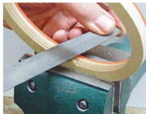
12 All the levels can then be cleaned up using a file to remove the bridges
