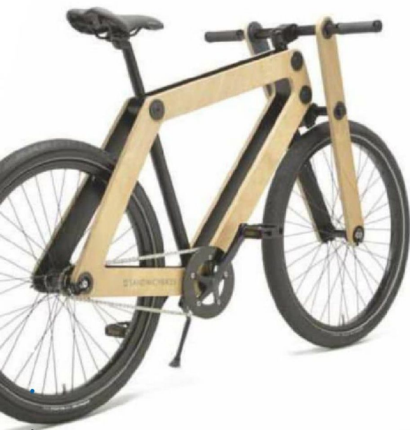
Sandwichbike, which can be assembled in less than an hour, features a wooden frame harvested from a sustainably-managed German forest
