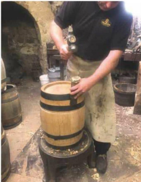
29 The belly hoop is driven down using a hammer and driver
