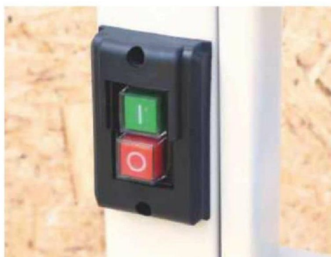
Sited on the neck of the machine, the NVR switch is easy to reach, its buttons shrouded against dust
