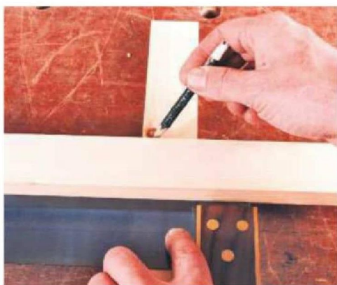
2 Use the mortise member along with the try square to mark the exact width
