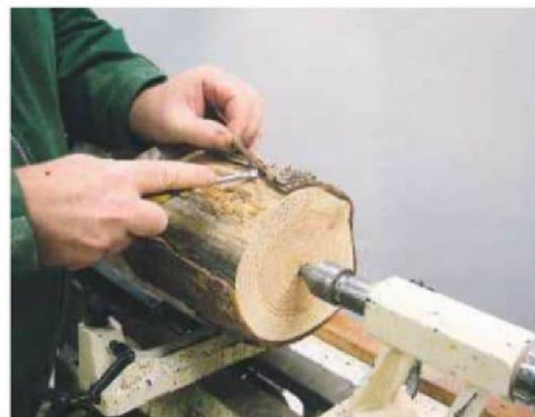
3 If the bark is loose, remove it before you start turning
