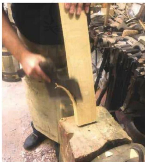
3 Listing the stave with a side axe
