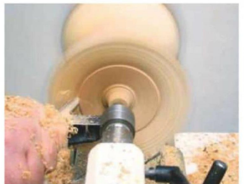
6 Mount the piece on the spigot and start to hollow at the tailstock end
