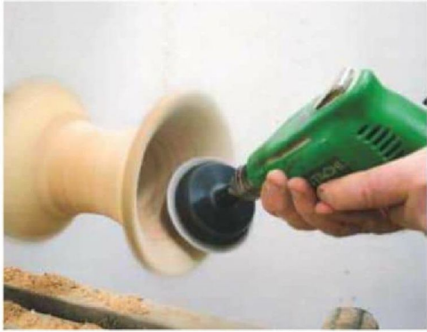
19 Once you're happy with the curve, sand this end to a finish
