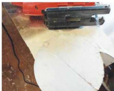
5 Ready to start jigsawing using a fine metal cutting blade
