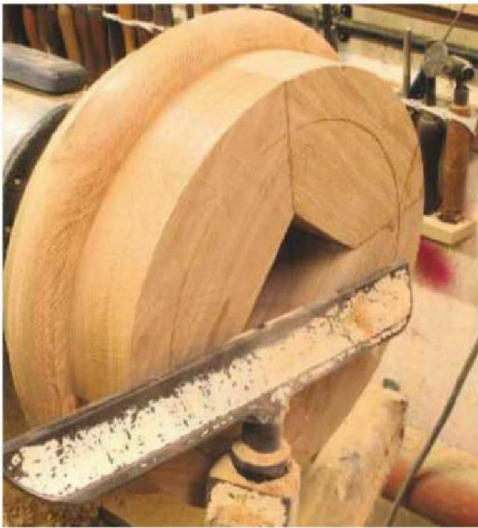
23 As I cut a spigot on the column before taking it off the lathe, I'm able to transfer this size onto the base's face. The hole up the middle will allow the project to accept a drain pipe, as mentioned earlier
