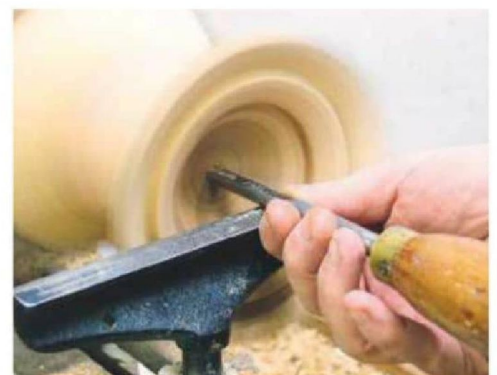
15 Use a spindle gouge to drill a hole right through the piece
