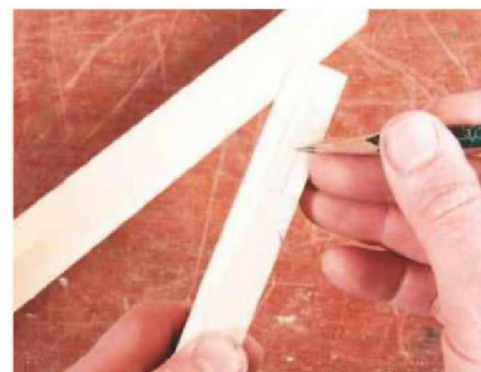
7 To make the marked lines more easily visible, run a sharp pencil down them
