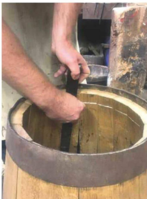
11 When sizing up the cask, a line is chalked around the inside, indicating where the groove will finish up
