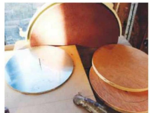
6 The perfect circle was achieved by slowly rotating the aluminium against the revolving disc sander
