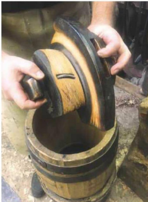
18 A chiv, used for rounding the cask ends, gives a perfect curve, before switching to a croze...
