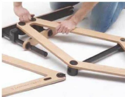
Sandwichbike, which can be assembled in less than an hour, features a wooden frame harvested from a sustainably-managed German forest
