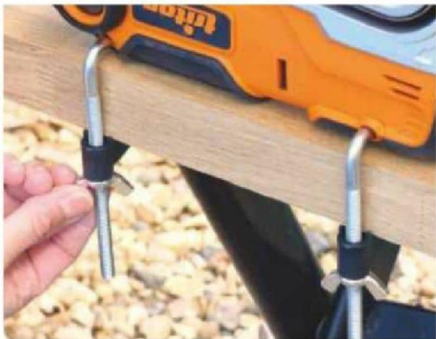
A pair of clamps are provided to fix the sander to a bench top, Workmate or even a scaffold board – up to a maximum thickness of 100mm
