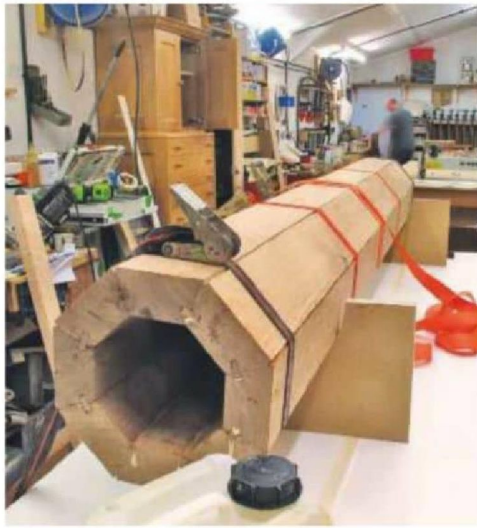
3 Clamping is really important and these ratchet straps offer the only practical method of holding the timber together while the glue dries. I've found that a good quality polyurethane glue is perfect for this type of work
