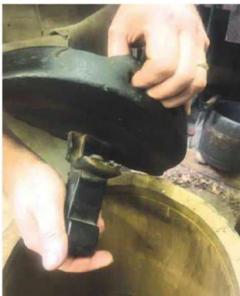
19 ... which is used to make a groove in the barrel head
