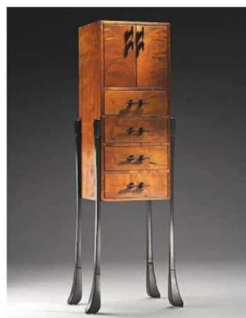
'Sterling' cabinet – 457mm wide × 1,219mm high × 305mm deep – solid orchard salvaged Claro walnut with ebonised ash pulls and legs. Features interior single adjustable shelf; all drawers are dovetailed and feature concealed hinges – finished with a hand-rubbed oil varnish blend
