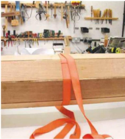
4 Always ensure you use enough straps and clamps. On this job, every 2ft seemed to be about right, with the glue just squeezing from the joints. If I'm feeling nervous about the joints, I'll leave the straps in place as I start to rough down the timber
