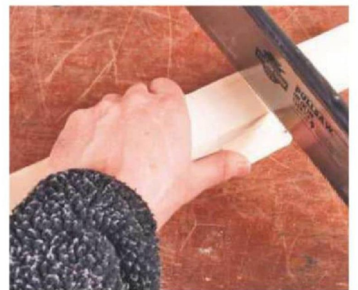
11 To cut the matching tenon, start by cutting the sides of the joint. Make sure the cuts are vertical and don't breach the depth line
