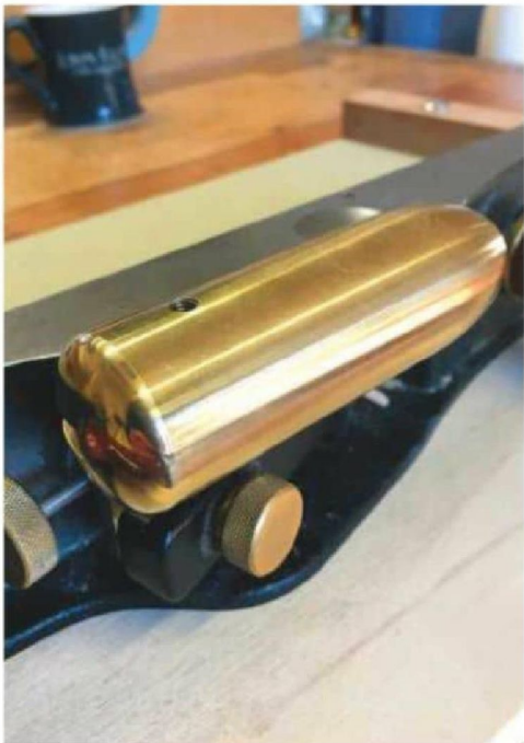
The flat end of the brass body gives the user another comfortable option to push against
