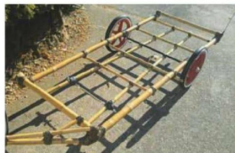
A bamboo trailer from Bound Bikes. Each trailer is made using varieties of bamboo, with joints made from plant-based epoxy (ecopoxy) with a choice of carbon, basalt, hemp, or salvaged jute burlap fibres
