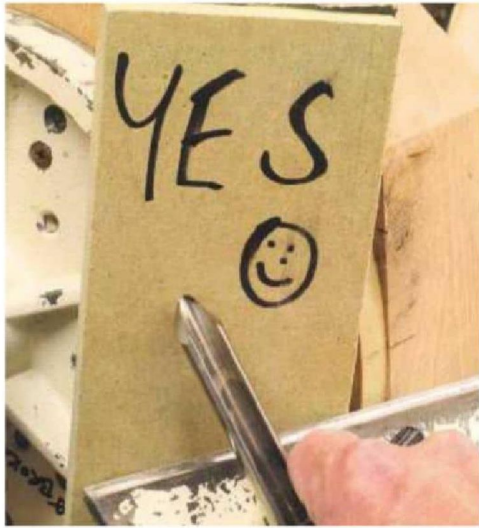
21 A 13mm bowl gouge is the perfect tool here. Be mindful of the wood splintering, which occurs due to the timber being laminated up. Work the timber just as you would a bowl blank
