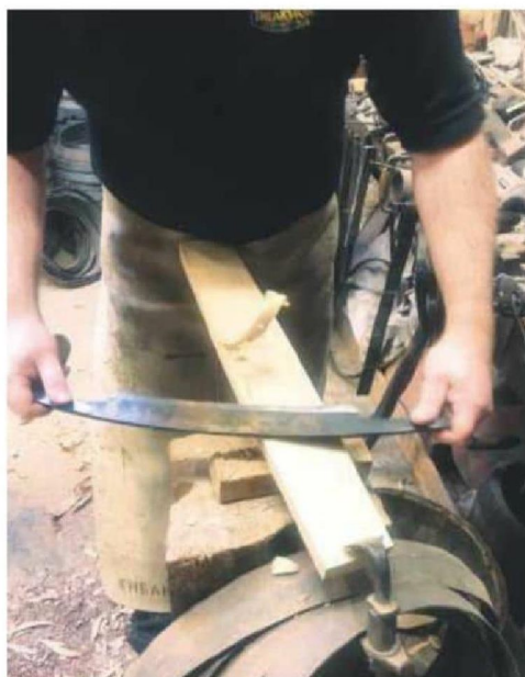
8 Backing the stave using a backing knife
