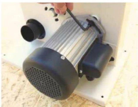
Changing to the slower speed of 460m per minute involves slackening off the motor retaining bolts...
