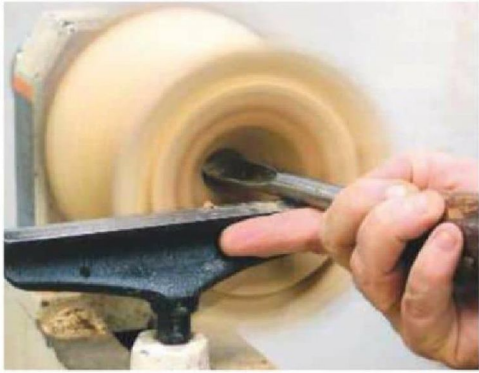
16 Widen the hole using a spindle gouge, working from the smallest diameter to largest
