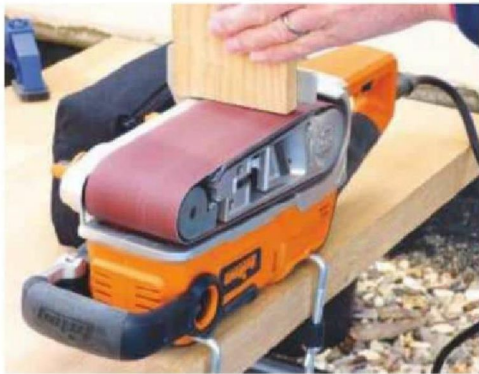
Unlike most belt sanders, the Triton is intended to be inverted, which really extends its scope
