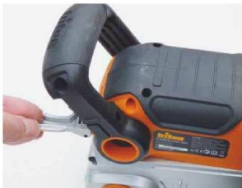
You can adjust the front D handle through 90°, simply by opening a small lever and clicking the handle to any of four positions
