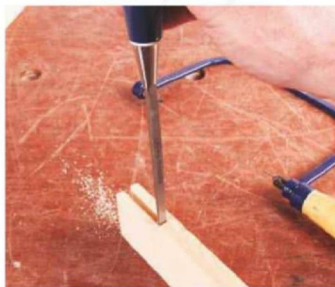
10 Square off the base of the slot using the chisel used to set the marking gauge
