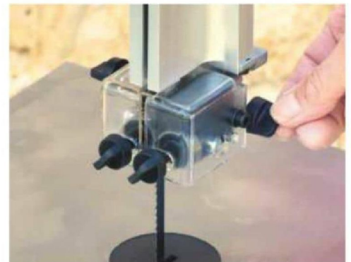
Roller guides above and below the table are spring-loaded, each tightened with thumbscrews
