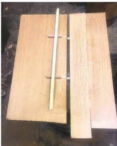
20 Preparing the heads. Timber held together with dowels, which will be cut on a bandsaw
