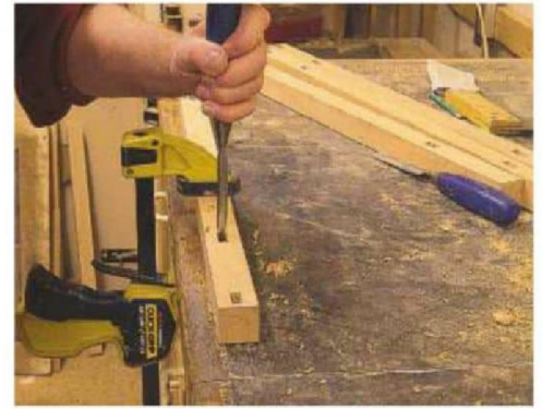
7 Cut the mortises to finished size using chisels. These will break into each other as they are cut into adjacent faces on the legs
