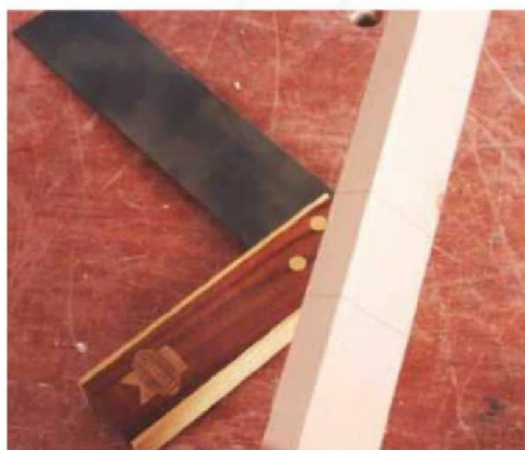
3 Extend the joint lines around the tenon member with a pencil and try square
