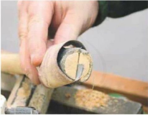
20 This photo shows my homemade sanding stick for narrow areas...
