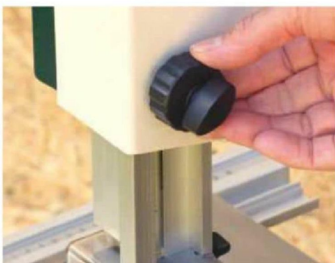
The upper blade guard is aluminium and operates via a rise and fall mechanism
