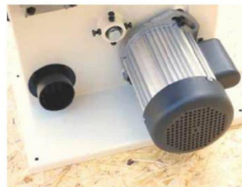
A 65mm port for connecting a dust extractor is located on the base...
