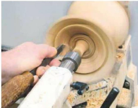
11 Cut a chucking recess at this end...
