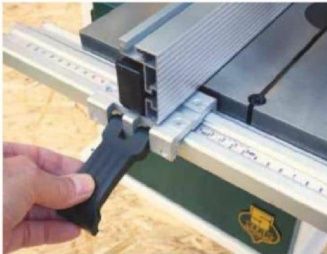
The box section rip fence hooks over the rail, and is locked in place with a large plastic lever
