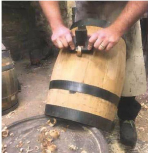
27 Using a downwright to clean up the exterior
