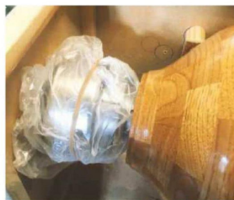
A sandwich bag and rubber band are all you need to ensure your chuck stays in tip-top shape
