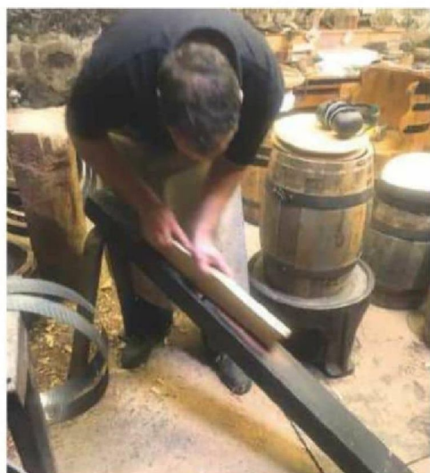
4 A jointer plane puts a bevel or angle on each stave
