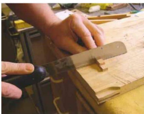
14 Having cut the step, part the button from the stock, then drill a countersunk screw hole through
