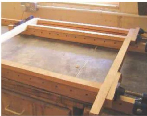
8 Having cut the joints, glue the front and rear frames together, being careful to ensure squareness
