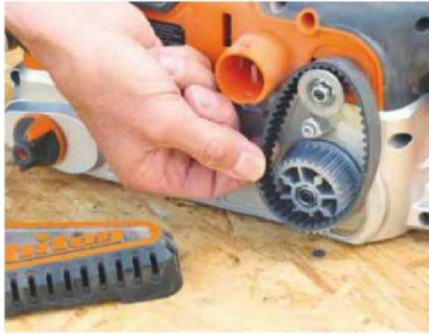
Access to the toothed drive belt is convenient by removing a screwed plastic cover, and a spare belt is also provided
