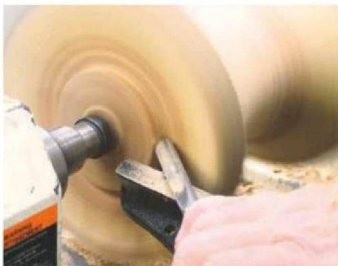
5 Cut a spigot to fit your chuck
