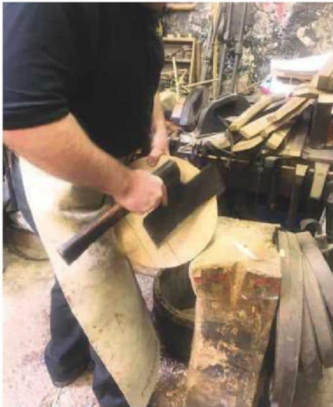
23 Using an axe to prepare the heads
