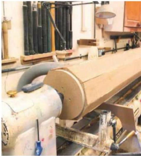
6 The Axminster Jumbo Drive is fine for work of this size, but I like to insert it into a 38mm hole, which ensures it has some support on the outer edge. In addition, I always use a live centre with a ring and a point, which provides extra stability
