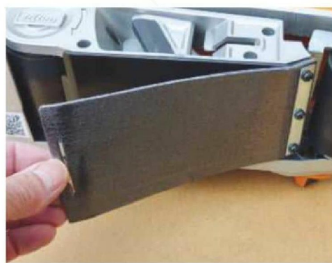
A graphite sanding plate reduces heat build-up, friction and increases sanding belt life
