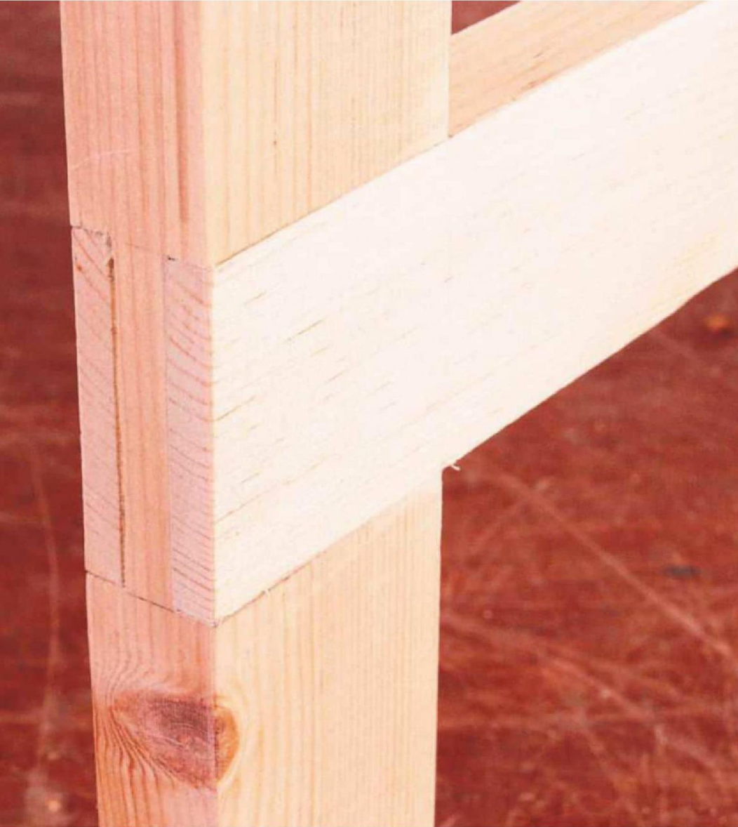
8 Fix the mortise member vertically in a bench vice. Cut down on the waste side of the marked lines with a fine-toothed saw
