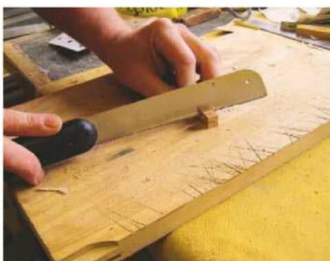
13 The buttons to hold the table top are prepared from square sections of timber. A small pull saw makes a neat job of removing the waste
