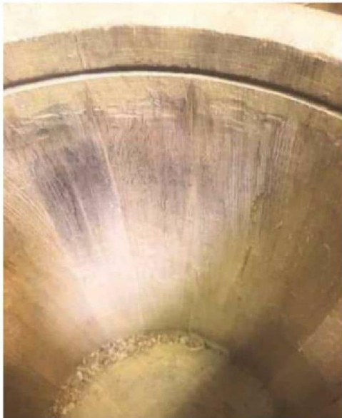
25 Looking down into the cask. A groove at the top indicates where the top head will be fitted
