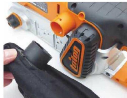
A zipped, fabric dust bag is provided, which twists onto a port on the left side of the body
