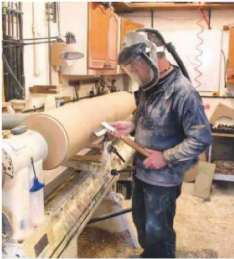
7 Off we go. On a piece like this, I keep lathe speed at around 250-300rpm. The spindle roughing gouge is locked to my side and the cut made by moving my body left and right. You can see how strong this makes the cutting edge
