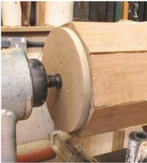
5 An octagonal section of timber, made to fit into the hole, was glued and screwed to a piece of MDF before being attached to the end. It could then be mounted on the lathe
