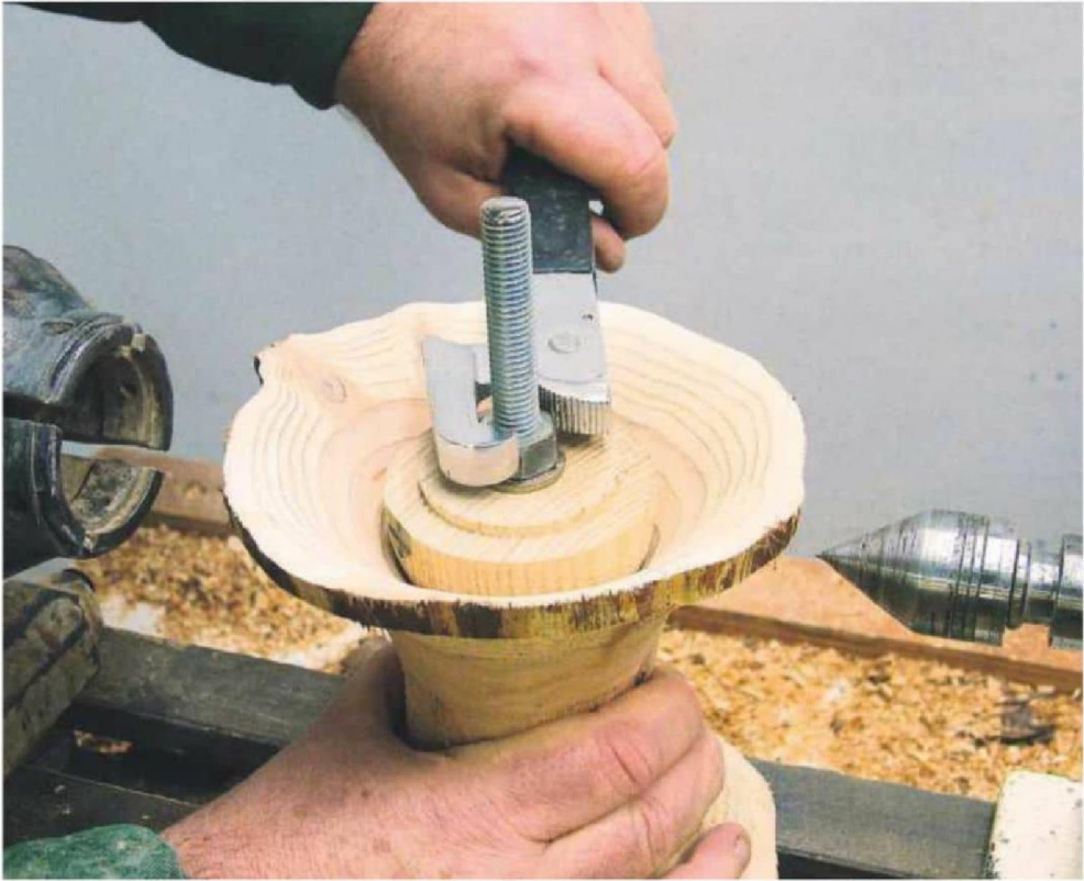
24 Tighten the workpiece between the two domes
