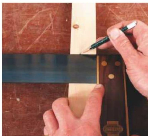
1 Start by marking out the joint with a try square on the tenon member
