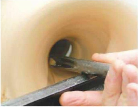
18 Keep the spindle gouge over on its side and use the bottom wing to make the cut
