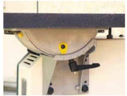
An all-important, adjustable stop bolt sets the table back to zero
