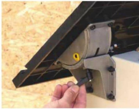
You can tilt the table up to 45° via a Bristol lever at the back of the machine
