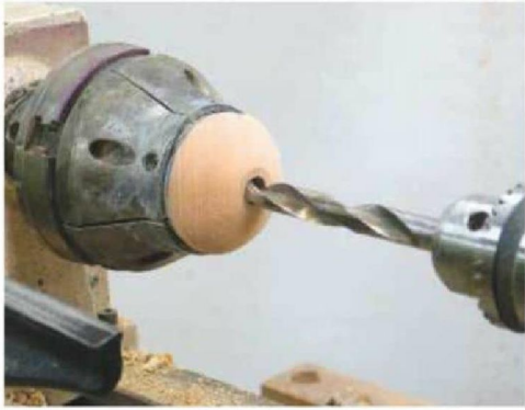
22 Make two domes with holes to fit your studding
