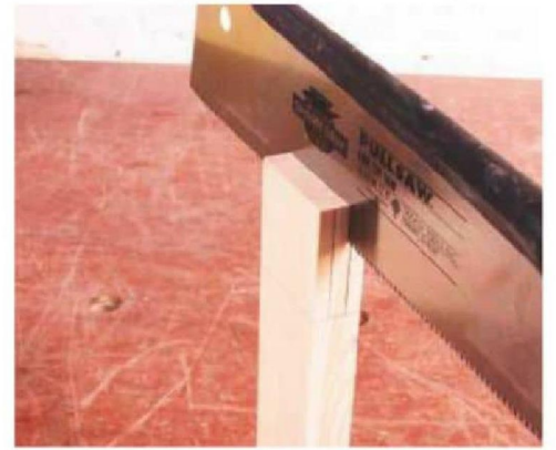
8 Fix the mortise member vertically in a bench vice. Cut down on the waste side of the marked lines with a fine-toothed saw
