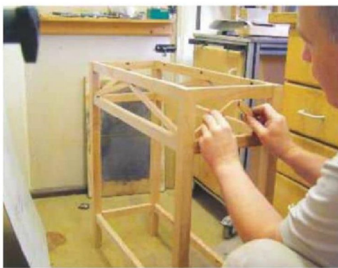
11 The infill rails are inserted in pairs, and hold each other in place while the glue dries
