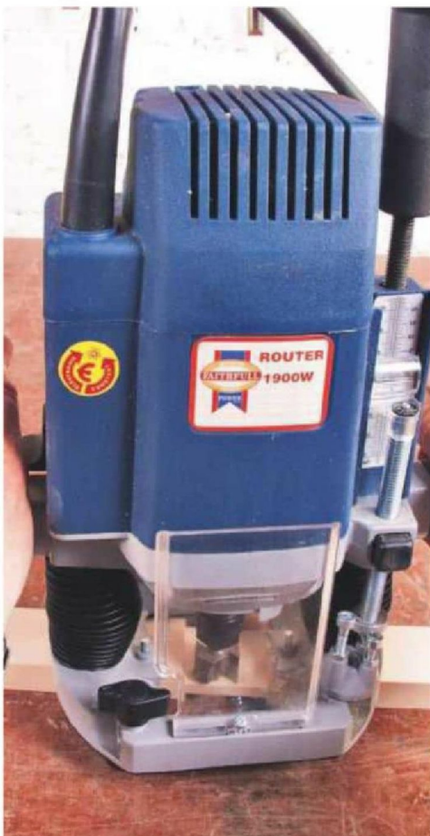
12 A router will remove most of the waste. Fit a wide straight cutter and plunge down to the gauged lines in stages. Be careful not to tip the router over the edge, and run as close to the sawn edges as possible
