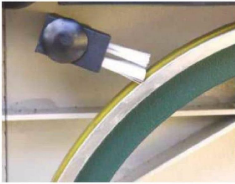
... while a small brush next to the lower bandwheel helps remove debris
