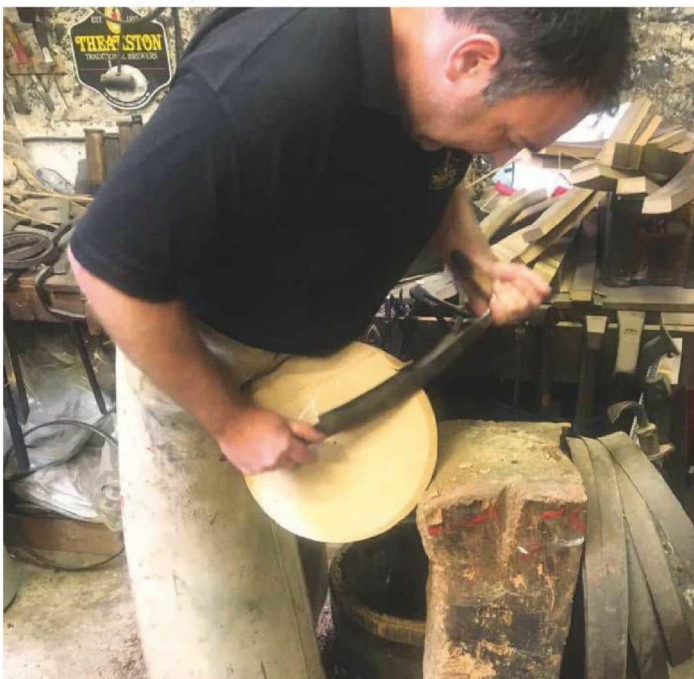
22 Work continues on the cask head
