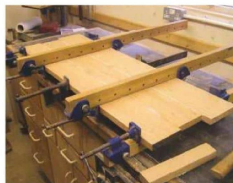
3 Cramp the boards together, alternating each side to equalise the cramping force
