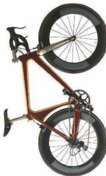
Selva Ti XXII road bike – the company takes pride in its unique glued-up wood shaping and use of different wood species to create striking veneer laminates
