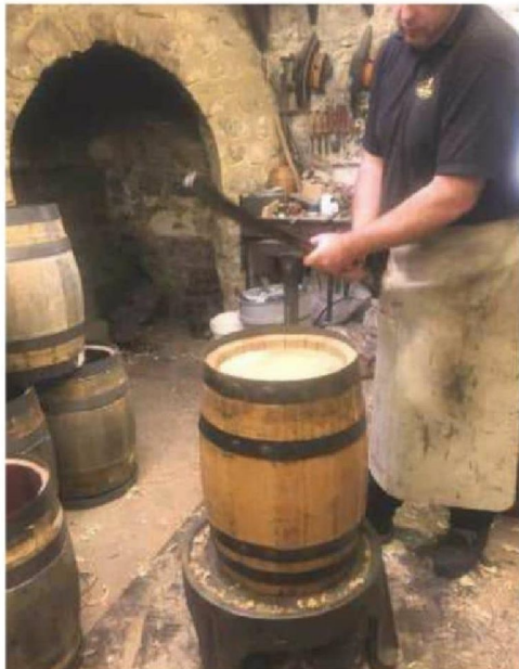
30 A cooper's bar is used to put the end hoops down
