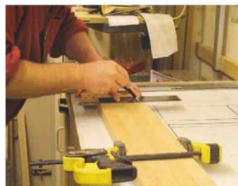
4 Having planed the legs to size, clamp them together and mark positions for the joints
