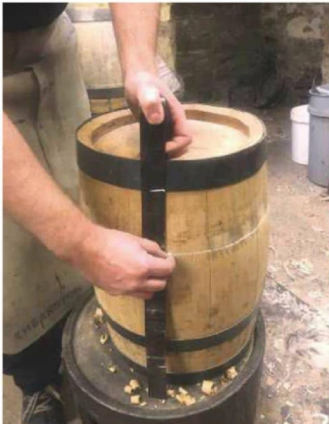
28 Marking for the belly hoop
