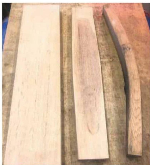
2 Stave blank, listed stave and bent stave
