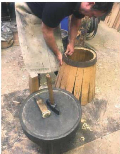
10 Raising up the cask with hammer and driver both visible
