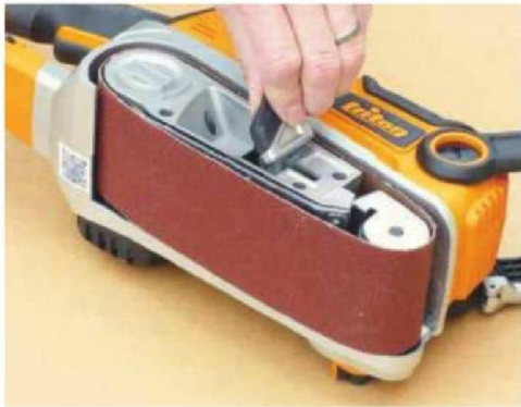
To change a belt, you open out the hefty sprung tension lever between the two rollers
