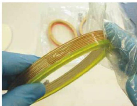
13 Applying a CA glue seal
