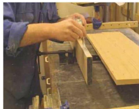
2 Edge-joint the boards for the top with a rubbed joint. Apply glue to one edge, which then needs rubbing against the mating part
