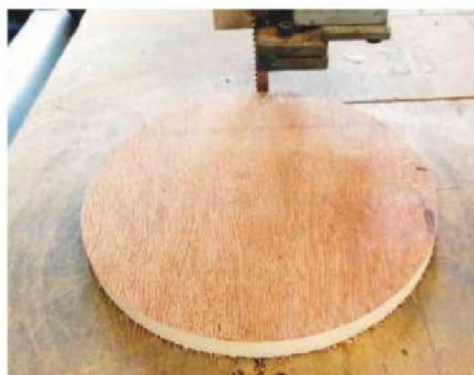
7 Using the ancient circle cutter to cut one of two 180mm circles
