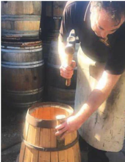
13 Cask raised up and almost ready for bending
