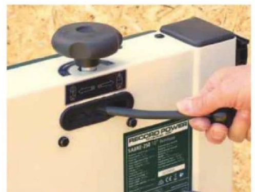
To change the blade, you first release the tension via a lever at the back of the bandsaw...
