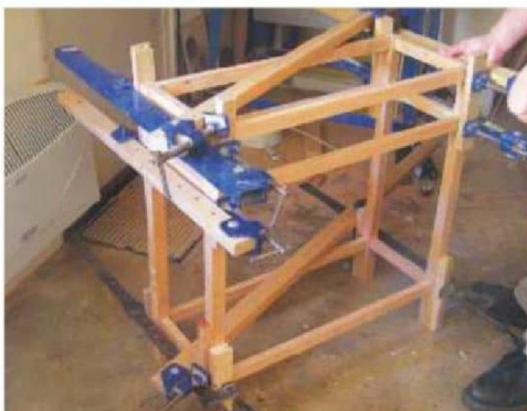
9 Join the front and back rails together with end rails. Use a clamp across the diagonal to keep the frame square
