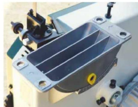
Initially, the table must be bolted to the cast alloy trunnion, which is easy enough with four M6 bolts
