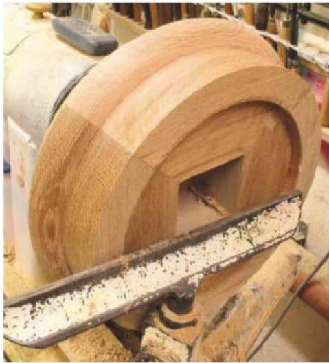
24 The bulk of the female part of the joint is removed using a gouge, in the same manner as you'd hollow a bowl. The sides are trued up using a round skew chisel, or bedan tool
