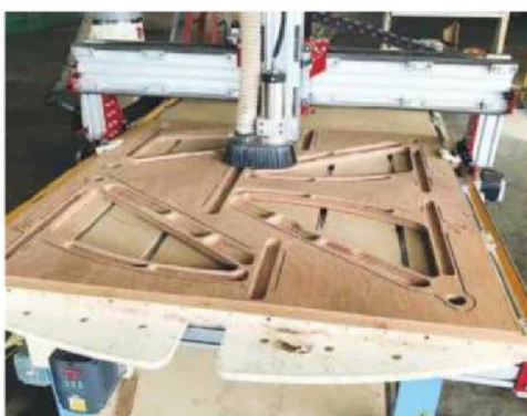
Bespoke wooden bike making at Pev Labs using a CNC to mill the bike frame contours and pockets
