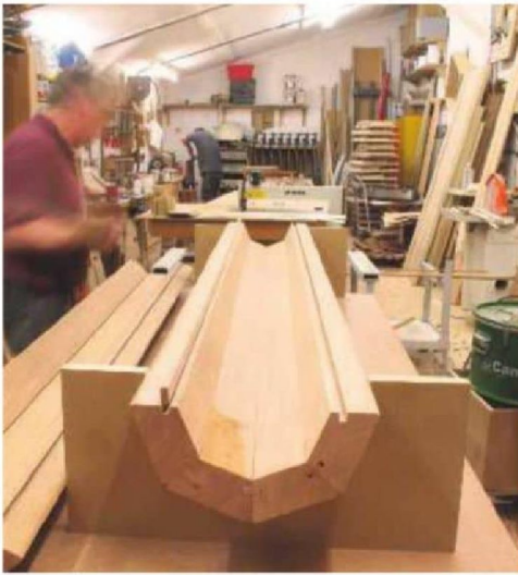
2 Here, Stephen is using a cradle to hold the columns. The loose tongue makes the joint much stronger. As well as increasing the gluing surface area, it also aids construction
