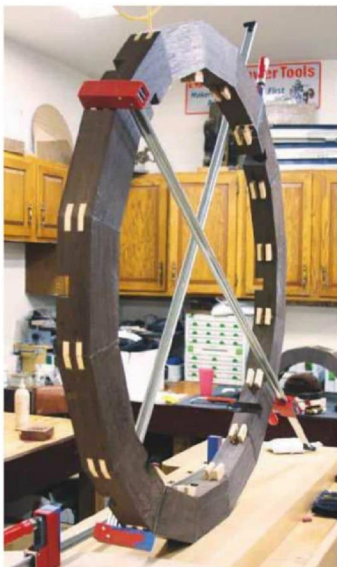
Close-up of spline joinery used for the 'Roundabout' table's segmented inner and outer rings
