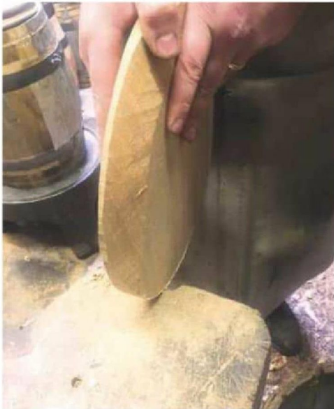
24 Side view showing heads being prepared
