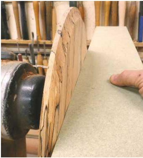
10 A nice straight piece of timber can be used as a guide to show how flat the bottom is. Mark the high spots with a pencil so you can see them when the blank is spinning
