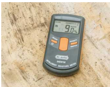
A pinless moisture meter in use
