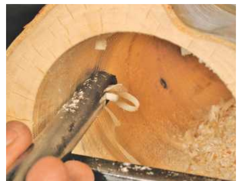
8 Finishing the inside of the log using the reverse edge of the Supertip 2000
