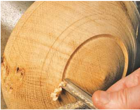
9 Use a bowl gouge to add the conical slope to the bird box roof
