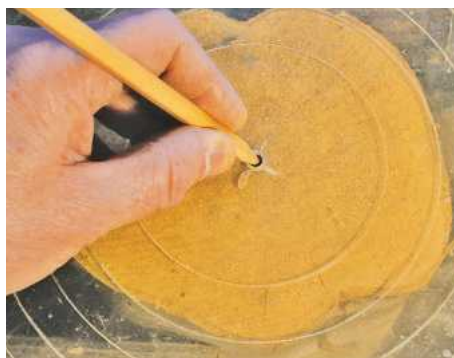
1 Find the centres at each end of the log and mount securely on the lathe
