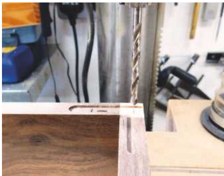
10 Drilling out for the hinge arm
