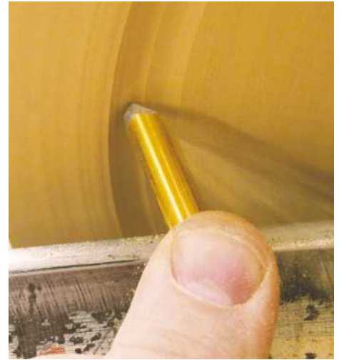
15 Turn the blank around and begin to hollow out the platter, starting with the rim. At this stage, leave as much stock as possible in the centre; this will stop some of the vibration that is experienced when turning thin
