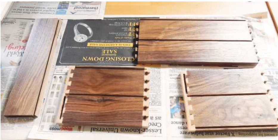
4 Inside finished and ready for assembly
