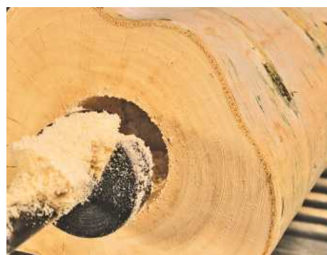
4 Use a large-diameter sawtooth bit to bore out the centre of the log
