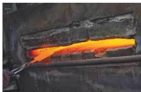
Heating a spindle roughing gouge prior to shaping
