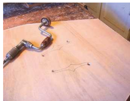
6 Each 'f' hole end is started with a different sized bit
