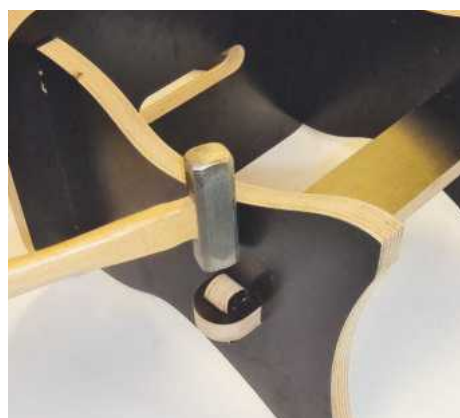
10 The tenons are tapped into position
