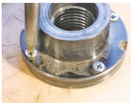
3 Attach a faceplate to the trued-up end; I used four Spax screws
