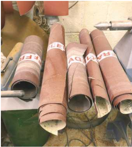
13 Having my brother's cabinetmaking workshop next door has many advantages and these used sanding belts come in handy for many turning projects, especially as the edges often haven't been used
