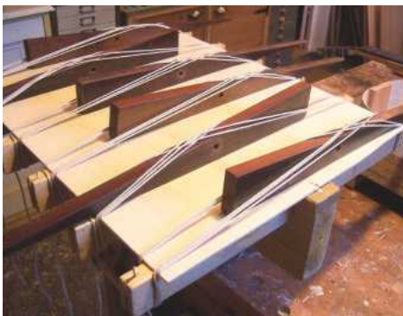
10 The soundboard is joined in a wedge and lace jig
