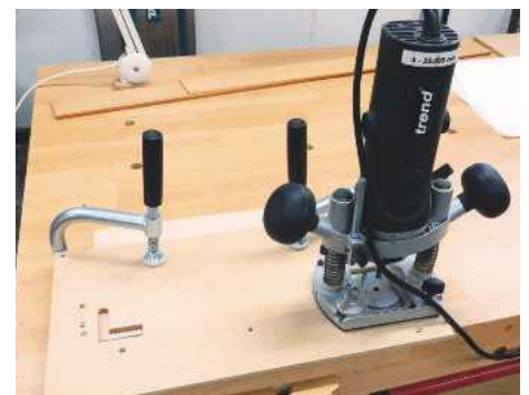
8 Routing the hinge recesses in the lid
