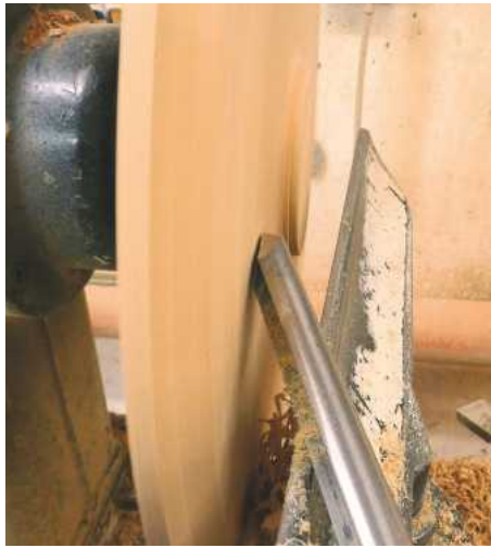
11 One of the easiest techniques to remove small amounts of material is a scrape with a bowl gouge. The flute of the tool is pointing at 3 o'clock with the lower wing in contact with the surface of the blank
