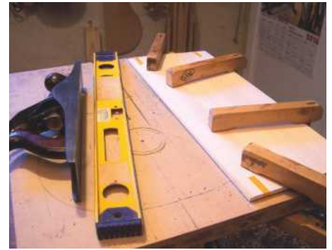
9 The soundboard edges are squared
