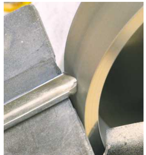
18 A good tool for cleaning across the bottom on the inside of the platter is the 60° bowl gouge. To sharpen, rotate it on the grinder platform
