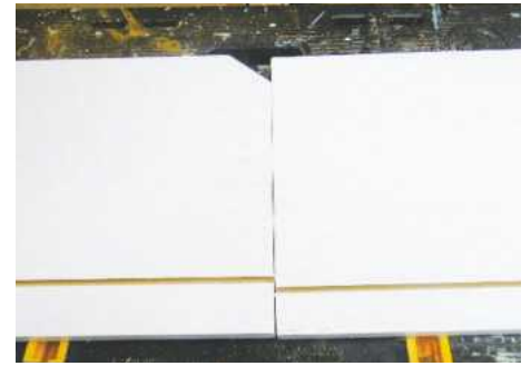
12 Groove detail for the drawer base
