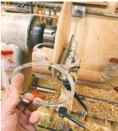
16 Regularly check the thickness of the piece using a pair of figure-of-eight callipers. Here I am aiming for something around 8mm; any thinner and the platter would probably fall apart
