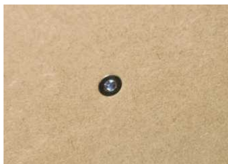
8 Confirmat screw in place
