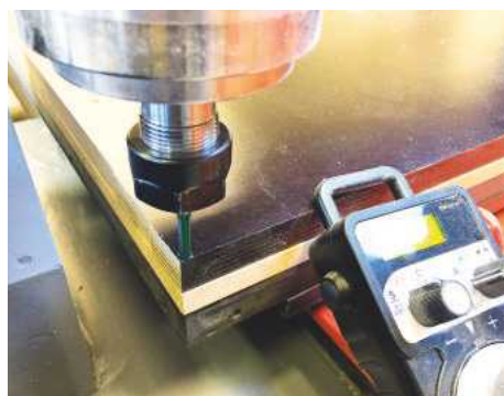
8 The start-point is zeroed using a remote controller
