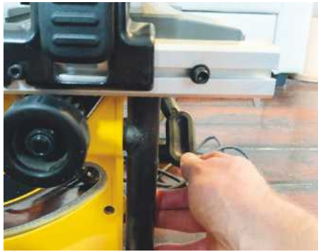
The measurement locking system is activated by pressing a lever
