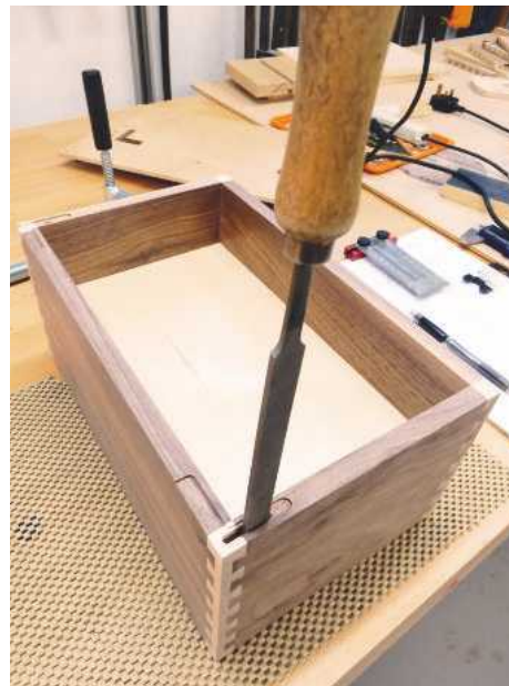
11 Cleaning up the hinge arm recess
