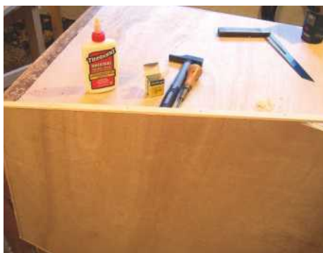
1 The edges of the soundboard are squared and faced with flat moulding
