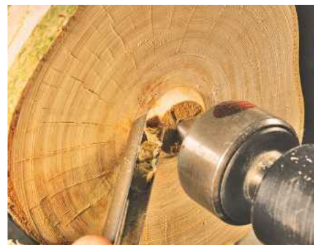
2 Slice one end of the log flat using a gouge or parting tool
