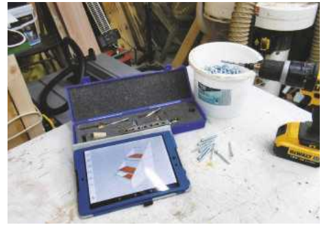
4 Joint Genie jig and Confirmat drill
