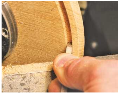
10 Cut a groove all round the edge of the underside to form a rain drip groove
