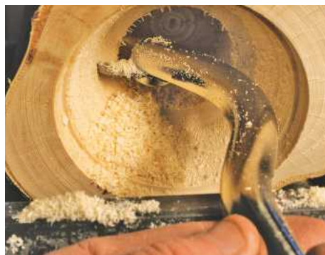
7 Option 3: Working with the swan-necked Hollowmaster; note the long overhang
