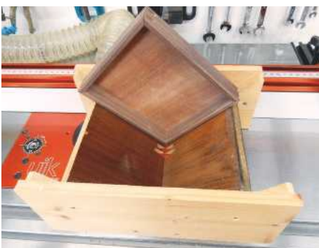
22 Routing the tray corners for splines
