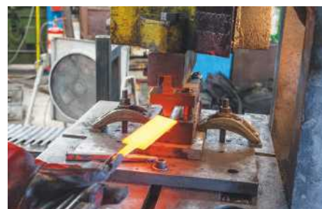
A spindle roughing gouge ready for pressing into shape
