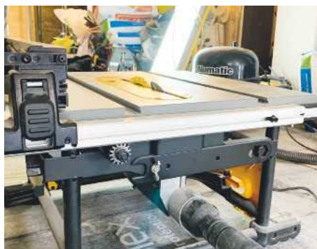
The main extraction, which exits from the back of the machine, pushes 90% of the sawdust from cutting
