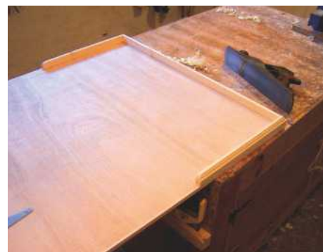
3 The rear safety rail is fitted
