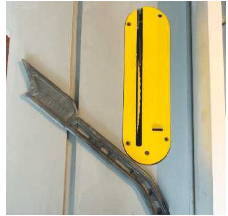
Aerial view showing the supplied push stick and 210mm diameter blade
