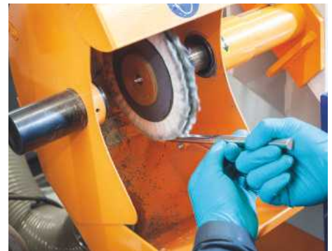
Polishing a spindle gouge flute
