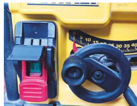
Close-up of the blade change wheel
