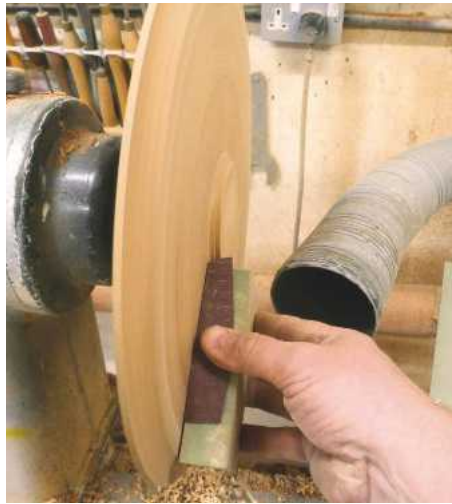
14 A piece of quality 100 grit abrasive on a wooden block is perfect for flattening off any small discrepancies on the base. Once I was happy with the shape, I power sanded the rest through the grits down to 400
