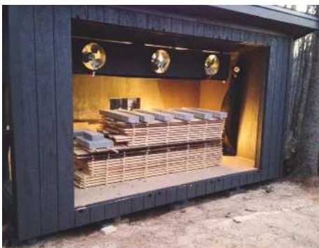
Drying wood in a kiln
