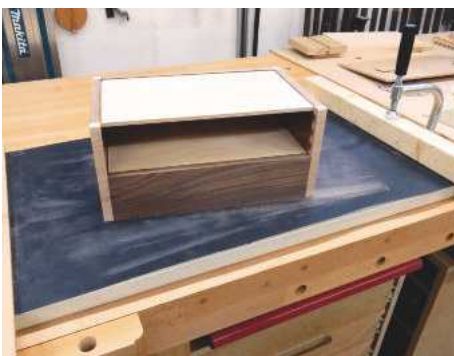
6 Flattening the top and bottom edges
