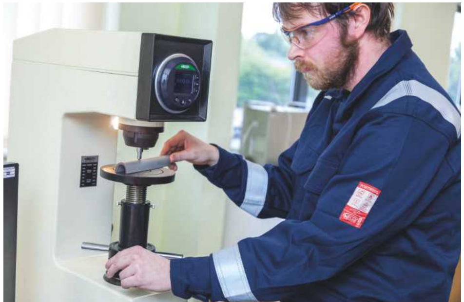
Tools are tested to ensure the correct levels of hardness
