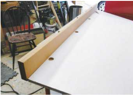
19 Marking the hinge positions
