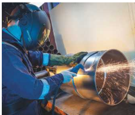
Plasma cutting a CamVac extractor drum
