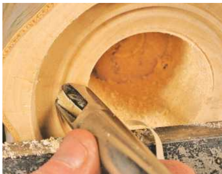
5 Option 1: Using the Supertip 2000, fitted with the Loop Hollowing Tool tip
