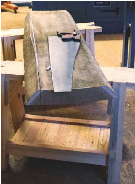
6 With a good saw and a couple of saw benches, hand ripping your stock doesn't have to be a pain
