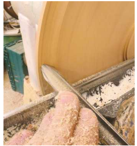
12 Once the bottom is as good as you can get it, you need to decide what to do with the rim. Half a cove is a simple but effective shape on the edge. This is cut with a bowl gouge, making sure the bevel is in contact with the surface
