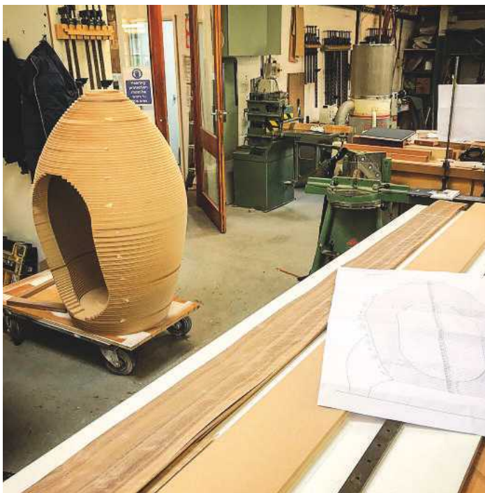
99 rings make up the body of the rocket
