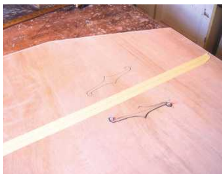
5 The 'f' holes are marked out
