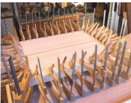
11 The soundboard is cramped onto a frame – note the centre strengthening strip
