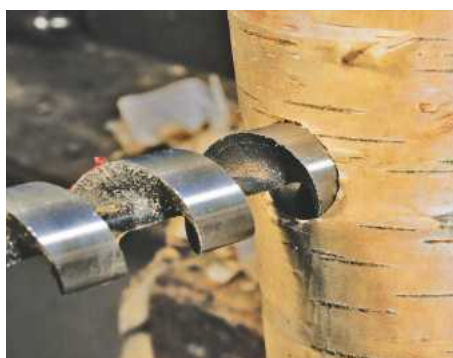
13 Bore out the entrance hole; a 25mm diameter is ideal for blue tits
