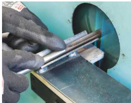
Polishing the outside blade profile
