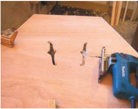
7 The 'f' holes are cut out with a jigsaw
