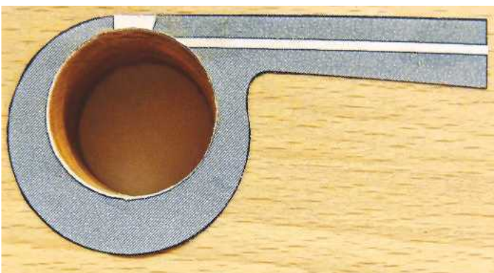
4 The hole for the chamber is drilled using a 22mm Forstner bit
