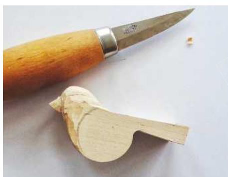
10 Using carving tools of your choice, cut around the template to reveal the bird shape
