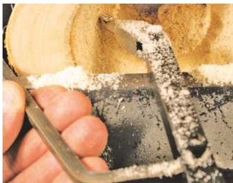
6 Option 2: Hollowing the log using the BCT Versatool Hollowing System
