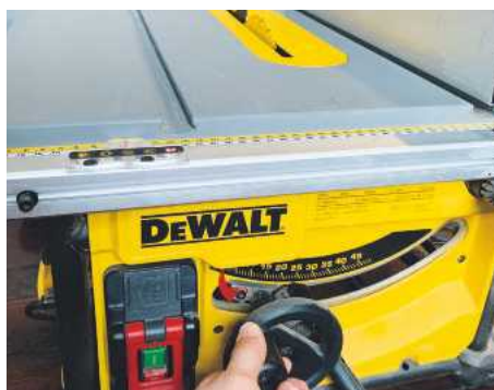
Blade depth is changed using this wheel on the side of the saw
