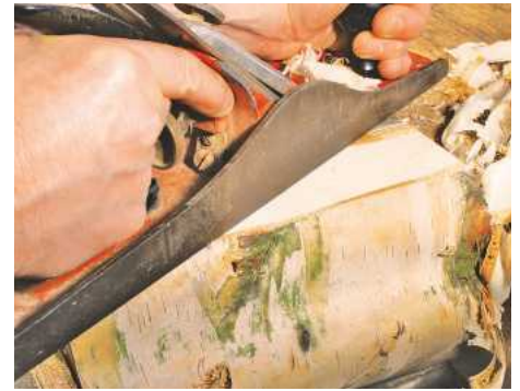
11 Plane a flat area on one side of the box so you can attach the backplate
