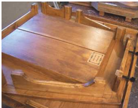
14 The folded podium held closed with two viola pegs
