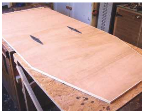
2 The platform halves are hinged
