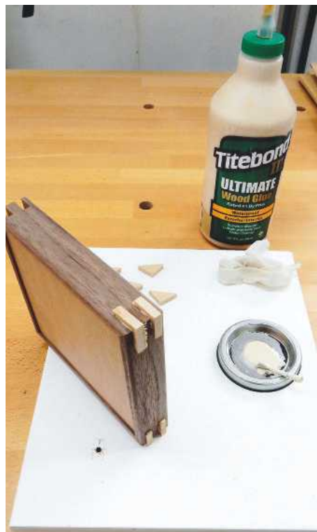
23 The oversize maple splines are glued in place...
