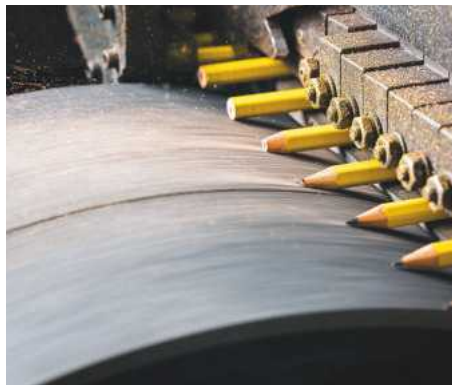
Inside the factory of General Pencil – one of the last remaining pencil factories in America. Here pencils are sharpened by rolling them across a high-speed sanding belt
