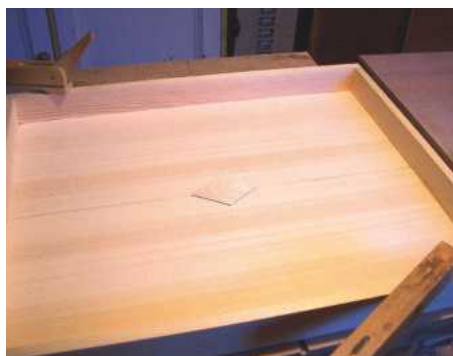
12 The cleat that will make contact with the soundpost
