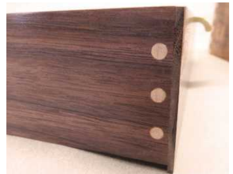
20 The drawer front held on with maple dowels
