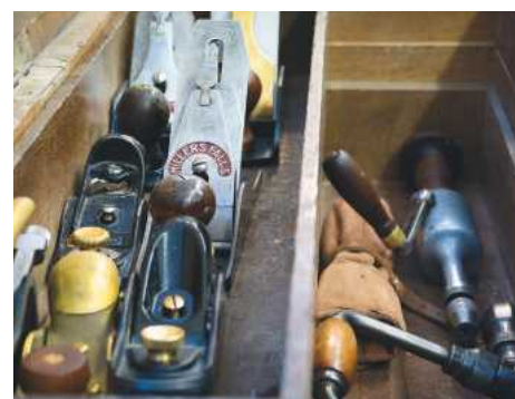
4 Build or buy a tool chest and keep the lid shut when you're not working; it'll help keep out the damp
