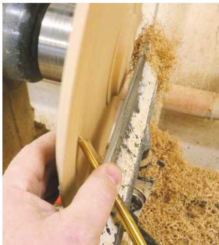
17 An option for turning thin is to support the work behind the cut with your fingers; this is a technique that should only be used if you're experienced in bowl turning, however
