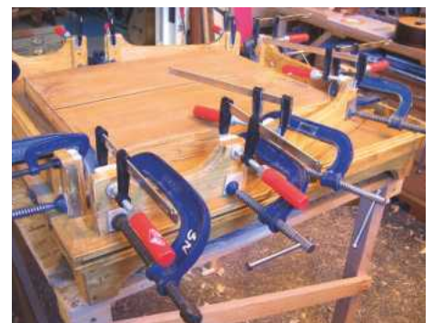
13 The legs on the support rails are strengthened
