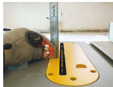
Squaring the blade on the table saw – this must be checked prior to use
