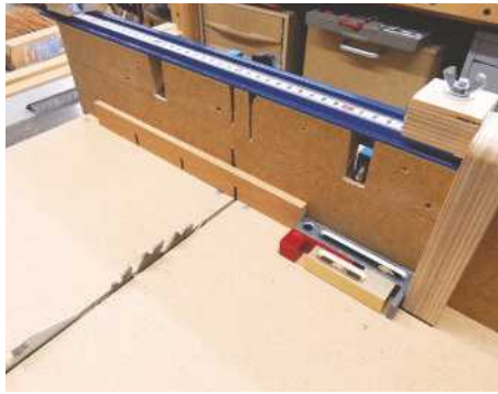
27 Cutting slots in the beech dividers
