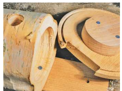
14 Cut a notch in the edge of the roof and fit it in place on the box
