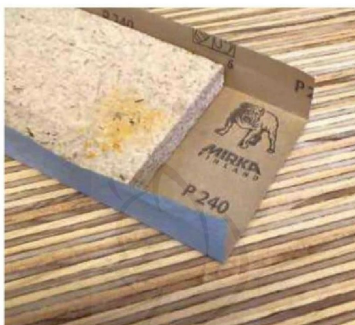
11 No visible evidence of sanding marks
