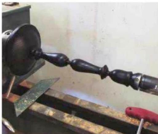
20 Mounting the candlestick between centres on the lathe means your hands can be kept off the work while applying the gilding wax
