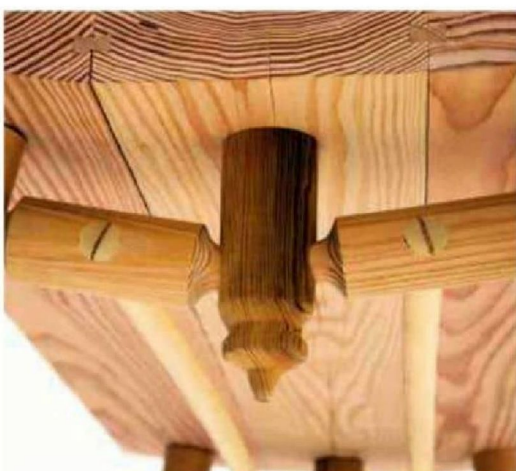
10 The two stool support rails fit between the pairs of short turned end rails, and run the full length of the table
