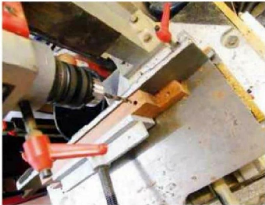
15 Drilling the two axes together ensures that both sides line up
