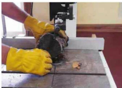
2 Cutting out the shape requires using a bandsaw
