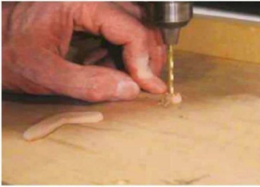
14 Drilling the holes for the mounting pins
