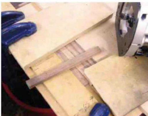
23 A simple jig cuts accurate rebates
