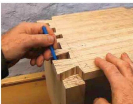
14 Use a clear and consistently accurate marker – a ballpoint pen
