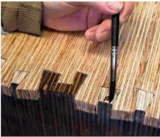
17 The tiny groove allowed for careful completion of the leg dyeing (after the pins are trimmed flush)
