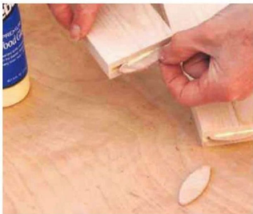
13 Cut slots for 10 biscuits in the door stiles and rails. Do a dry assembly, then glue the biscuits in place
