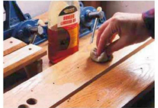
28 Applying linseed oil with a rag
