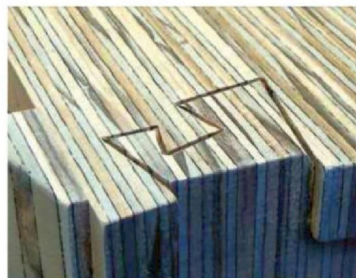
7 A routed 1.6mm groove highlights the joint
