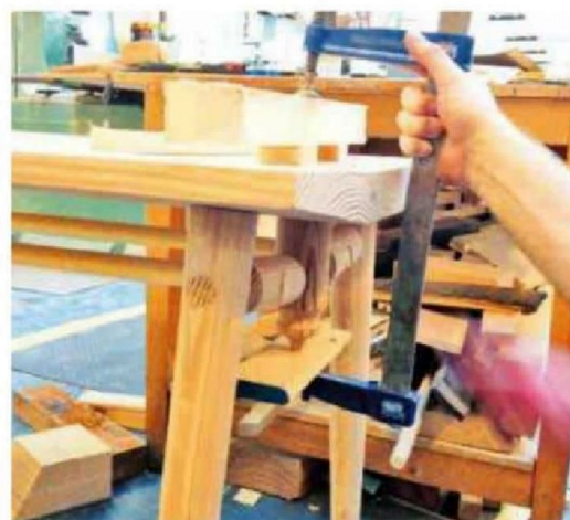
9 The underframe is assembled piece by piece. Finally, the turned central column is fitted into the table top and cramped tightly
