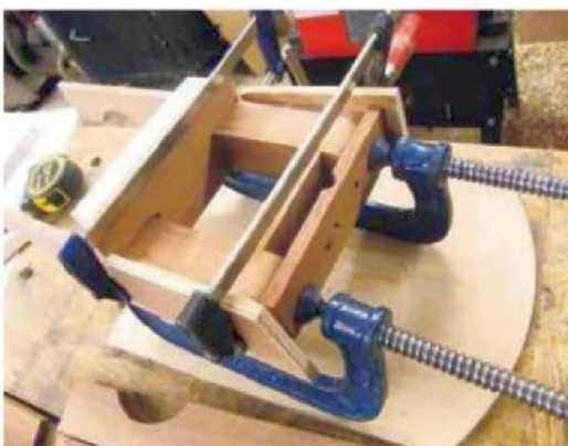
10 Use softeners when clamping and check all is square
