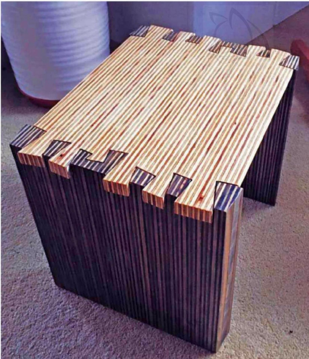
19 Subtlety in the design: the stack laminated plywood further expresses the edge in the dovetail sectioned slab ends and on the mitre sectioned top, which exposes very little of the bland surface veneer. Added to this, the reflection of light from a window on the top changes as you move around the room, highlighting the groove shadowlines
