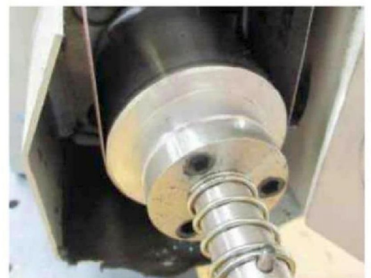
The carrier bolts to the powered spindle (I then vacuumed the dust!)
