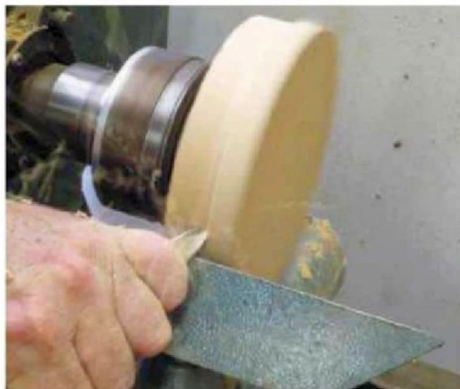
2 The bottom surface needs to be slightly concave...
