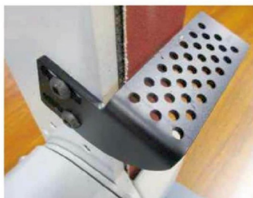
The toolrest can be used for freehand grinding of scrapers and gouges
