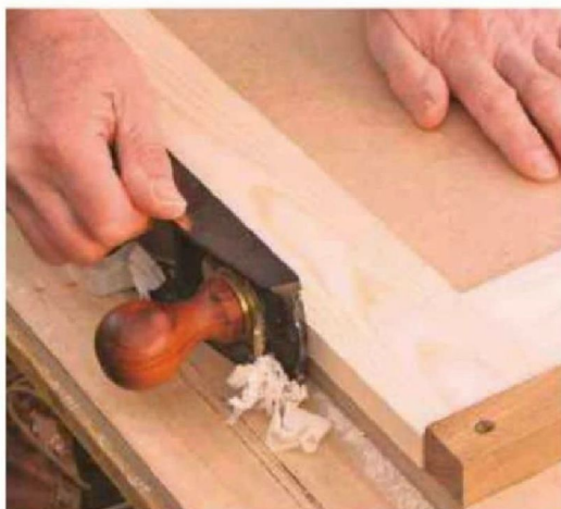
16 Plane the edges of the door to fit the carcass, allowing a gap of about 1mm all round
