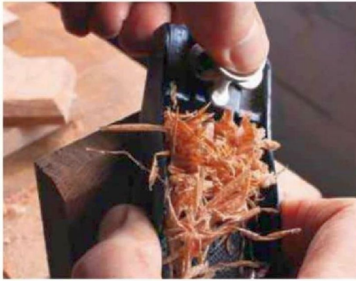
26 Chamfering end-grain with a low-angle block plane
