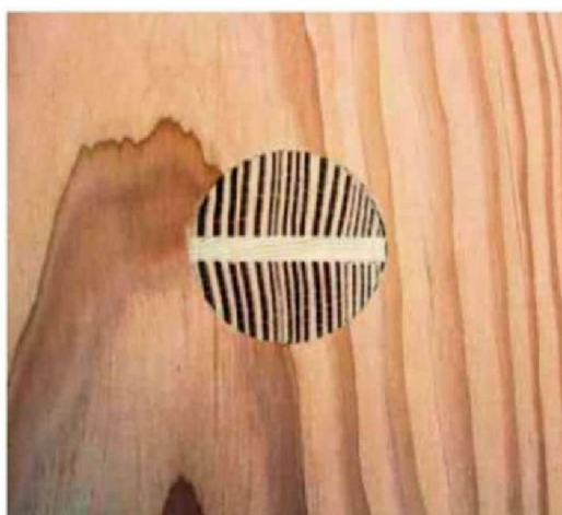
11 Every tenon in the set is locked securely into its mortise with a contrasting wedge; no glue is used anywhere in the assembly
