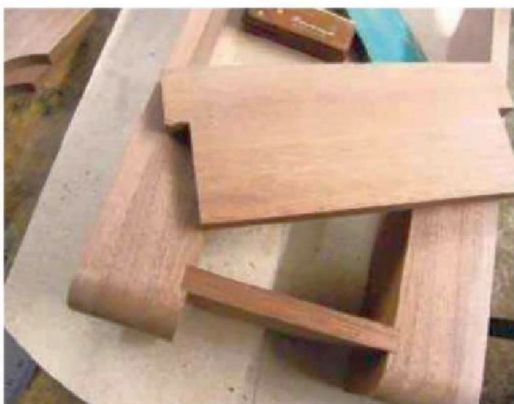
8 The dashboard is made to fit between the sides
