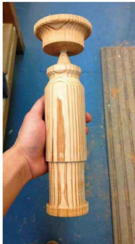
6 The narrower cylindrical part of this turned column will be wedged into a large hole bored into the table top
