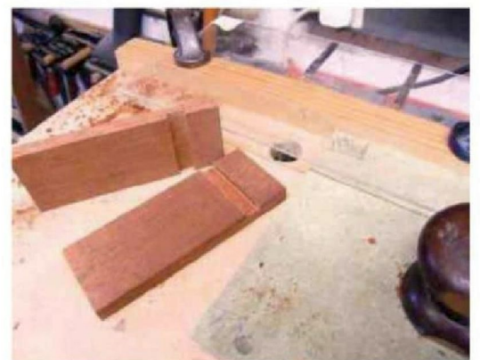
4 Note the use of an MDF push block to reduce any breakout
