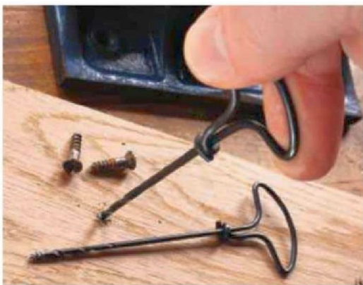
17 Making pilot holes for wood screws with the auger gimlet
