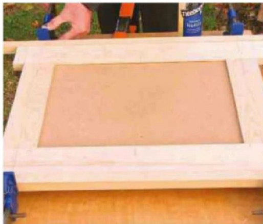
14 Insert the panel and cramp up the door on a flat surface, checking everything is square
