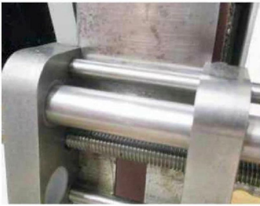
'Optional' honing guide is a necessity for sharpening plane irons
