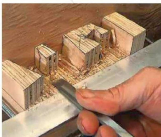
13 Avoiding plywood fibre breakout with a hand chisel was almost impossible
