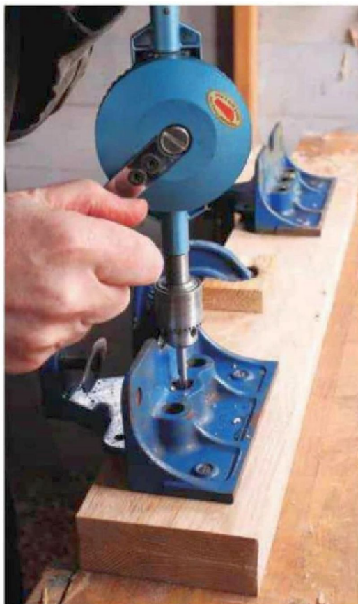
18 Drilling for guide bars with the Footprint 160A hand drill
