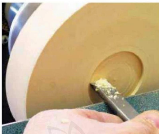
5 The dovetail angle must closely match the one on the chuck
