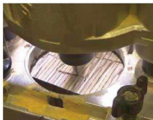
16 Using a batten guide, the routing of the 1.6mm wide groove is tricky
