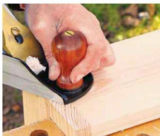
7 When the glue has dried, plane the end-grain of both sides flush with the top
