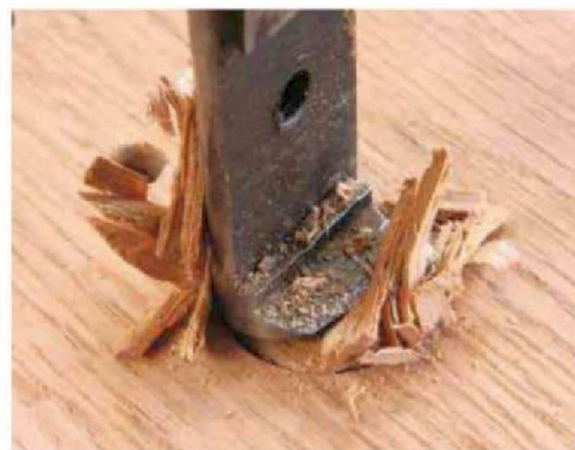
21 The bit's second spur leaves a tidy edge
