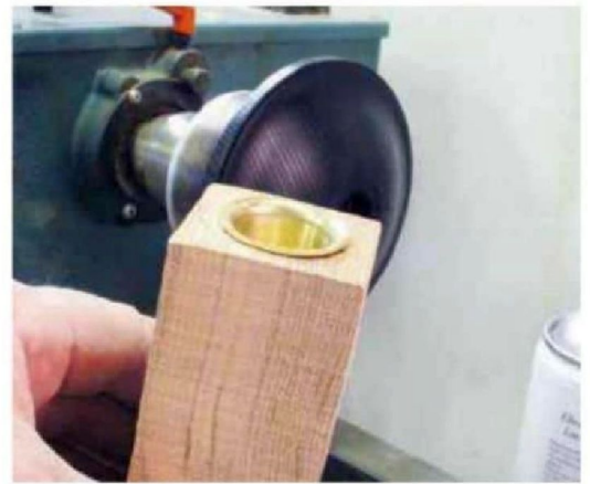
12 The large hole requires use of a large-diameter point on the live centre
