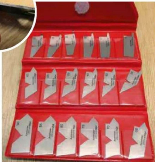
The universal gauge set is a good buy and helps you to check the bevel angles of tools
