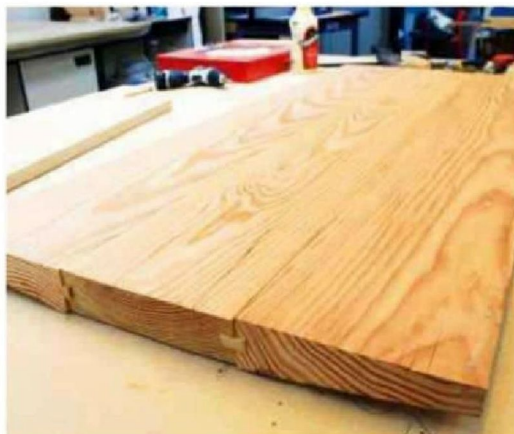
5 The three solid sections forming the table top are locked together with full-length dovetailed tongues for strength
