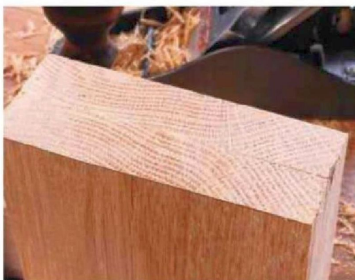
15 Planing ends together reduced the risk of splintering
