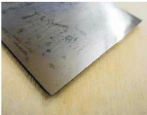
The mirror finish on a plane iron back
