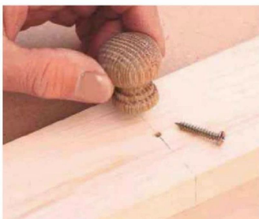
19 Mark the position of knob or handle on the stile and drill for a mounting screw. Counterbore from rear
