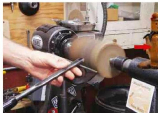
3 Using the bowl gouge with the lathe speed set low, begin to form the basic features
