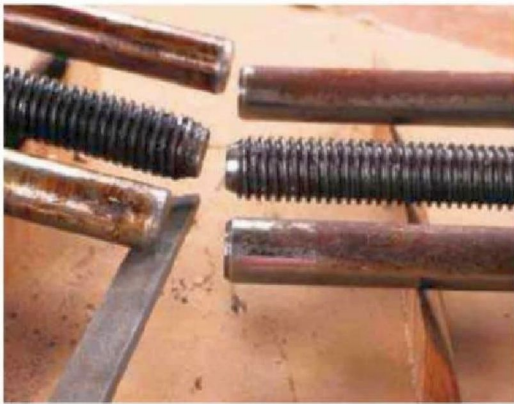
8 Mushroomed ends of guide bars were filed with a taper
