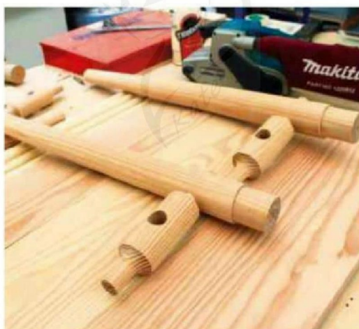
8 Each table leg will be linked to the turned column by a short rail that is drilled to receive one end of the stool rail
