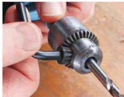
19 The hand drill's key-operated Jacobs chuck
