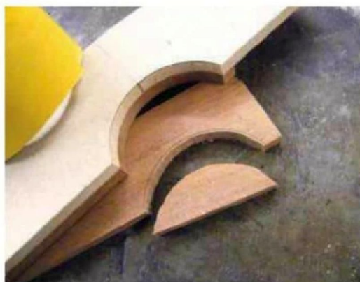
3 Note how the template is level with the lower edge of piece (A)
