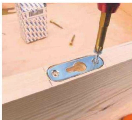
10 The cabinet is mounted on the wall with steel hanging plates. Rout recesses and drill screw holes
