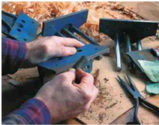
9 Vices dismantled for cleaning
