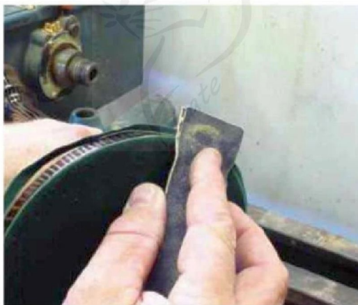
26 Cutting the baize with abrasive produces a neat result
