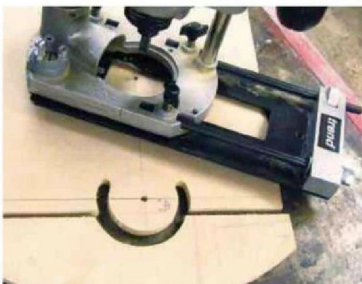
2 Make an MDF template using a circle cutting jig
