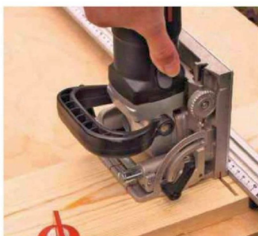
4 Mark out positions of joints on top, bottom and sides and cut slots with a biscuit joiner
