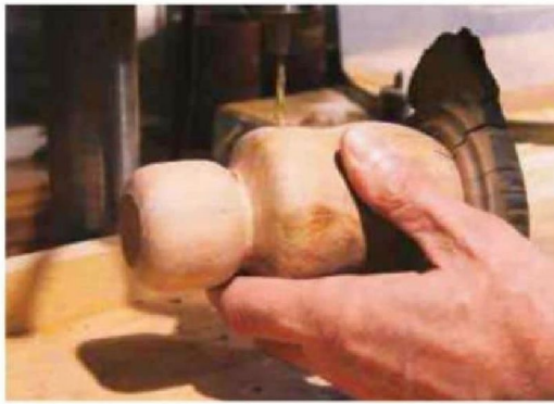
18 Drilling holes to accept the arms...
