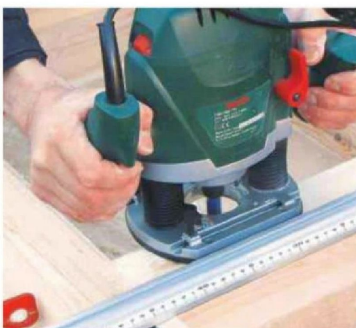
11 Rout a 7mm deep rebate for the MDF back panel. It's easier to do this before gluing up the carcass!
