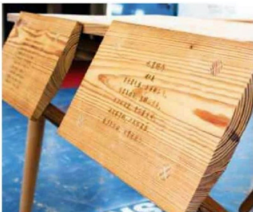
4 The stool legs are joined to each solid, chamfered seat with wedged mortise & tenon joints. Note the laser engraving
