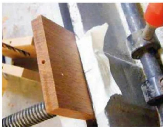
19 A piece of masking tape on the rear fence helps with accurate location
