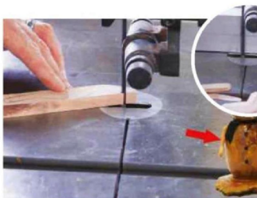
12 Cutting out the arms using a bandsaw
