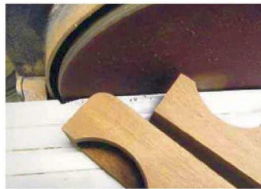
7 A disc sander made light work of this stage
