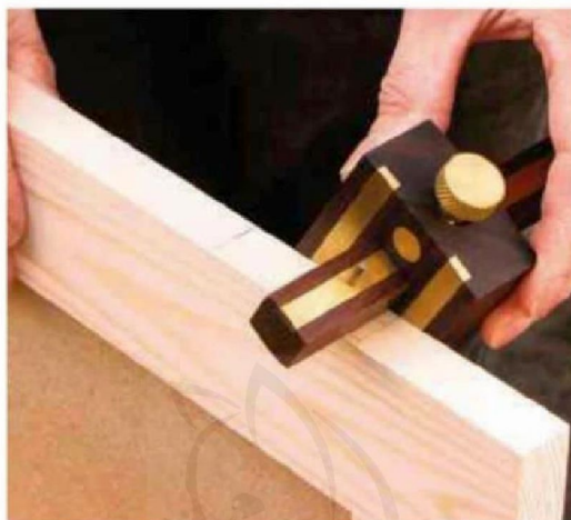
17 Mark positions of butt hinges on the stile. Flap ends should line up with the rails
