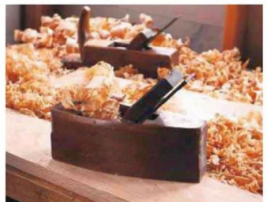
16 Face planing flat-sawn oak was a battle against tear-out
