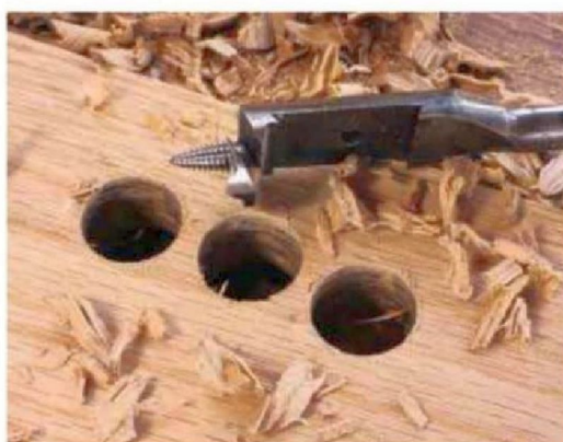
23 Clearance holes for the screw and guide bars
