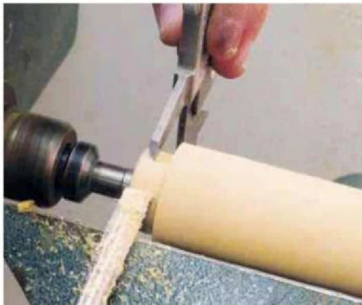
13 With the callipers set to the diameter of the base hole, the left-hand end is turned down
