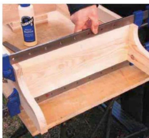
6 Assemble the cabinet with PVA glue, using sash cramps across the joints. Check for square
