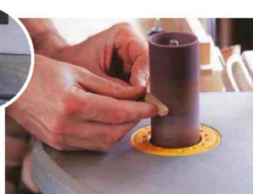
13 Refining the arms using a spindle sander
