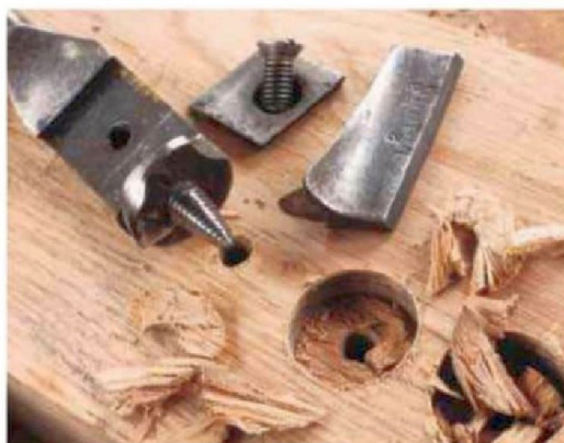
20 ConValCo expansive bit with cutter removed
