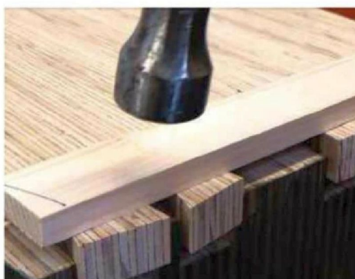
15 A hammer used (with protective scrapwood) has more impact than a mallet
