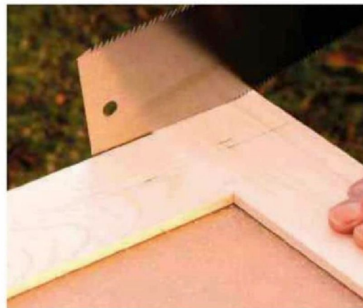
15 Saw off protruding horns on stiles, leaving enough to trim flush with a bench plane
