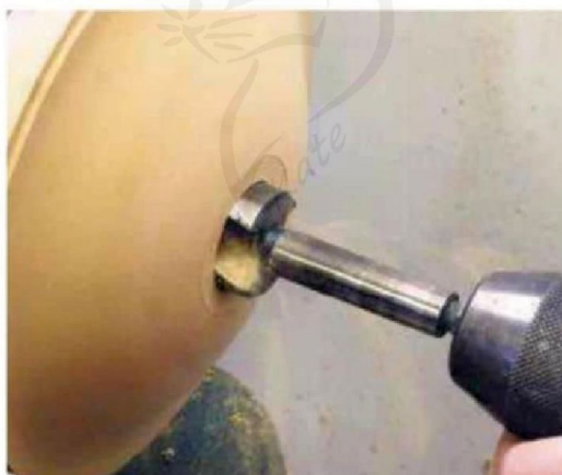
8 The hole for the stem is 30mm diameter
