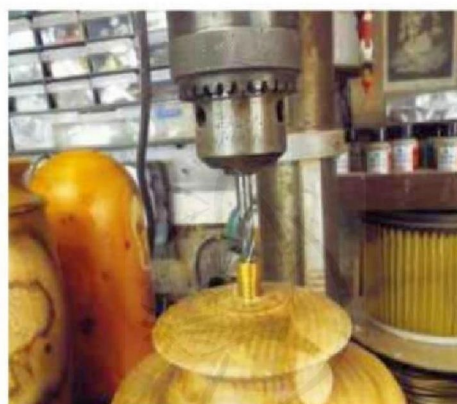
The brass nipple pressed into the base
