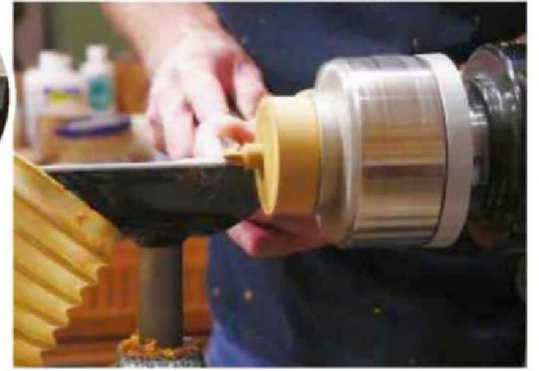
16 Turning the noses from scrap hardwood using a skew chisel
