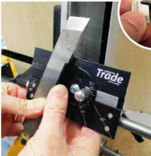
The universal sharpening table is not so good with skew chisels
