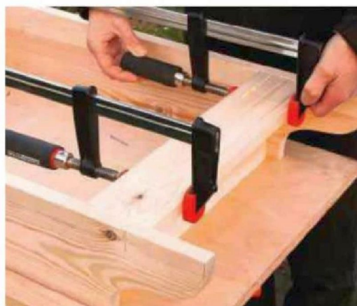
9 The lower apron is simply fitted to the bottom panel with biscuits. Glue and pin the sides
