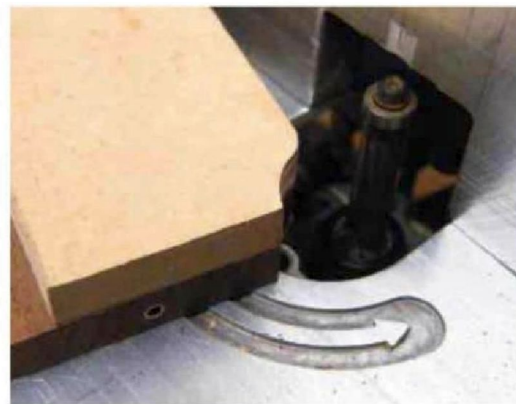
21 Trimming the corners to shape
