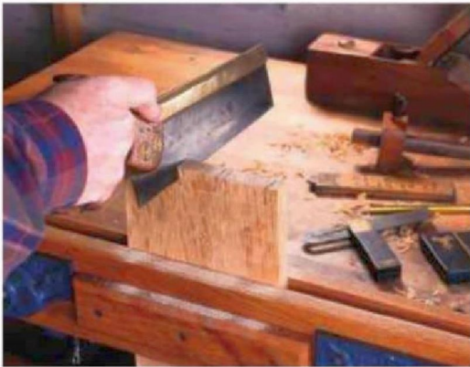
30 Sawing dovetails at a convenient height
