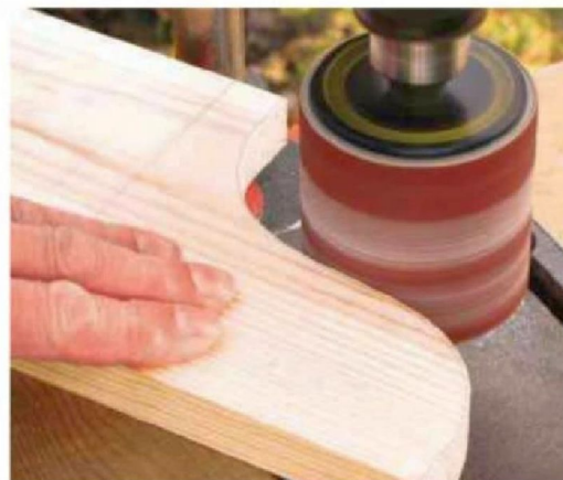
3 Clean up the sawn curves with a sanding drum mounted in a drill stand
