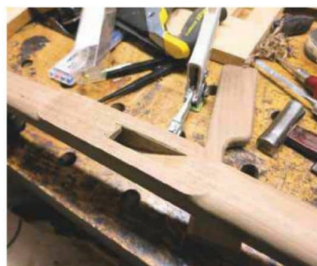
49 Rear leg slot after cleaning up
