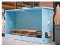
Kiln-drying wood using a Sauna wood drying kiln from Logosol
