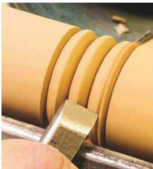
26 I'm using the skew chisel to form the beads. The long point slices through the wood with a small amount of bevel in contact, keeping the chisel going forward all the time
