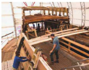
16 On the main deck up to 70% of the ship's timbers had to be replaced
