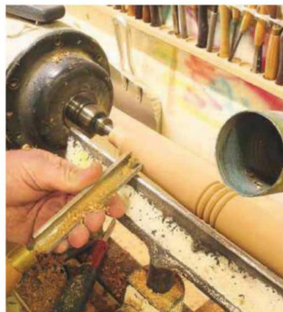
27 To make the legs look lighter, turn away some of the material to the left and right of the beaded detail in the middle, using the small spindle roughing gouge for more control
