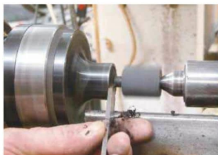
16 Bring the tailstock up for support while you turn the spigot
