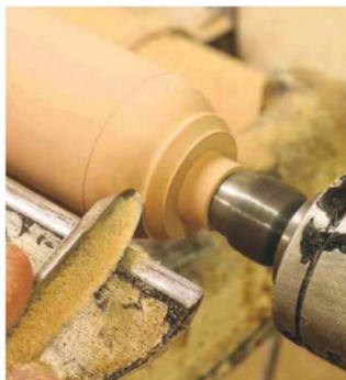
28 Shaping the bottom of the leg is carried out using the Signature spindle gouge. Roll the tool over to the right keeping the bevel in contact with the wood
