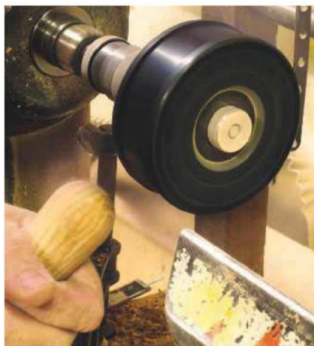
32 Once the waste on the ends of the legs is cut off they must be sanded. My Sand-o-Flex rotary sander is the best tool for this as it doesn't over sand the end-grain
