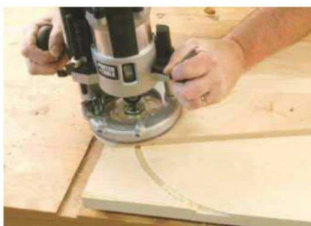
There are a variety of router jigs you can make yourself in the workshop
