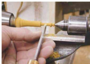
19 The pins are held in a chuck and supported by the tailstock while you turn them
