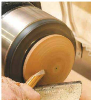
34 Once a chucking point is turned on the piece it can be held while the top is rounded over. I decided that a large button shape would look best
