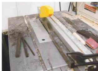
8 Cut the ebony on a tablesaw, using a push stick for safety
