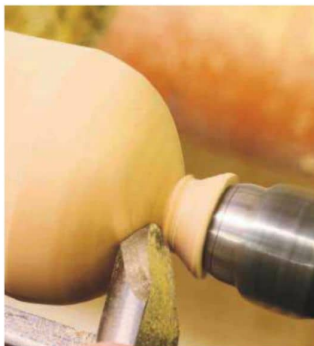
29 At the end of the cut the tool is right over with the flute at 3 o'clock. If the bevel came away from the wood and the point came into contact with it, you would experience a 'dig-in'
