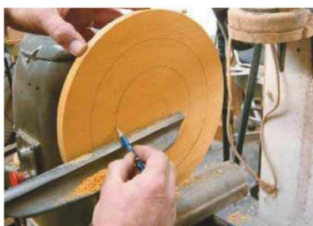
4 Mark off and pencil in the cut lines for the steps
