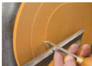
5 Turn the steps slowly, using a sharp parting tool
