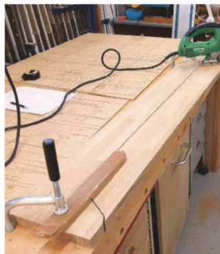
1 Shaping the rear support panel
