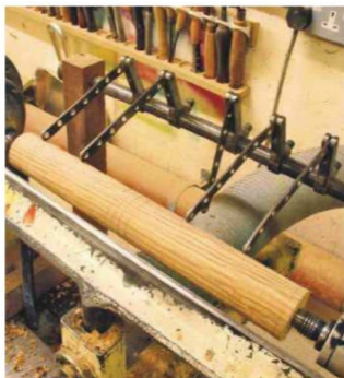
31 I use coping fingers to measure the next two legs, removing the wood until the fingers fall through; this is much better than using callipers
