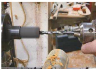
15 Drilling the holes for the ebony base blocks requires a combination chuck
