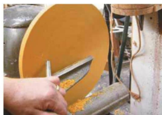
3 Keeping the lathe on a low speed, use a 9mm gouge to face up
