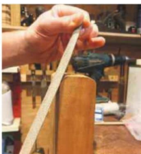
Using the finer No.9 to finish off the roundover
