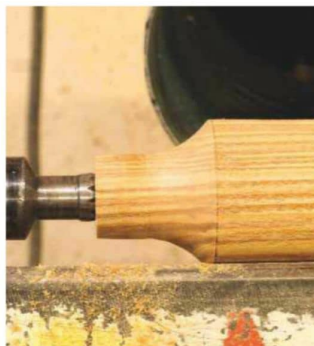
24 You can see how the cove flows perfectly into the spigot; the larger-diameter curve will hide the joint where the spigot goes into the base
