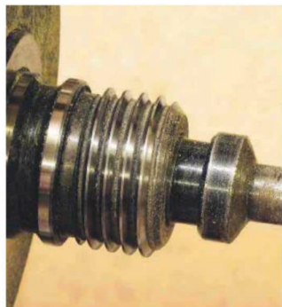
19 This is the small Steb centre available from Robert Sorby. They're not cheap but the spring-loaded point and the multi-tooth design make them the most effective of drives
