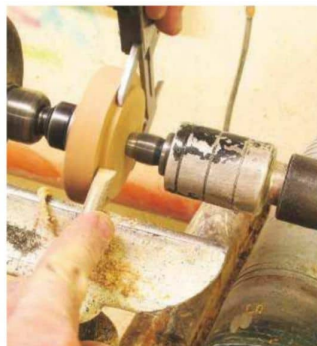
33 All that's left to do is turn the cap to go into the recess. A piece of ash from the same board is cut to size and mounted between centres
