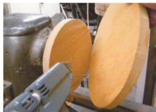
2 Hot glue the blank onto a scrap piece of wood – screws are a definite 'no'
