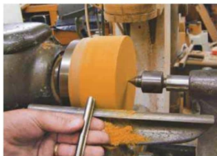
12 Glue the base onto scrap wood and turn it to the finished diameter
