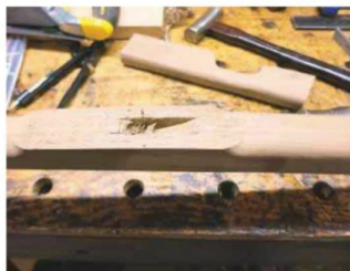
48 This hole is made using a 12mm chisel and matching drill bit
