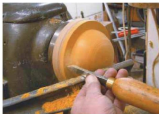
13 Use a parting tool to form the flat area of the base...
