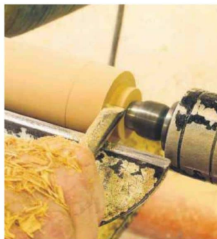
21 After making the wood round with the spindle roughing gouge, remove some of the waste from the tailstock end with a parting tool
