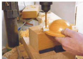
21 Drill the holes for the base with the pillar drill; set the depth stop
