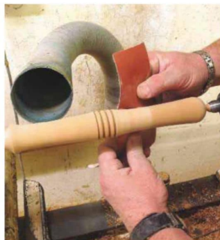
30 To see the shape more clearly and not sand away the detailing, I like to sand the wood behind like this. Be careful not to remove the spigot
