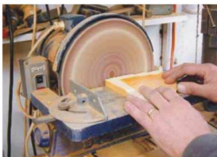
7 Use a disc sander to quickly sand off those edges
