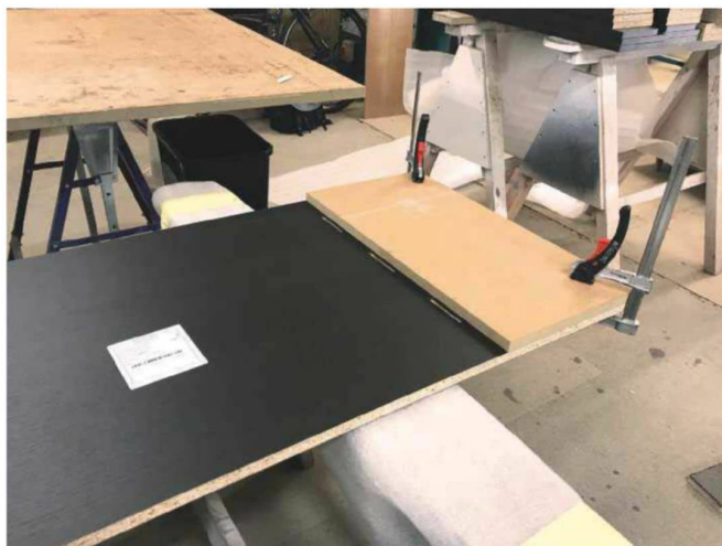
Laying out the locations for biscuits for a shelf in a carcass side using a template to locate spacing and distance from the top
