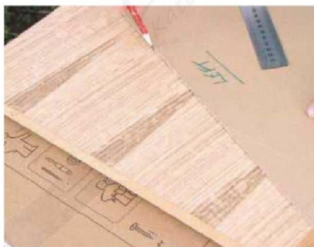
8 Select the best face for the top surface and draw around the template. Stick masking tape over pencil lines
