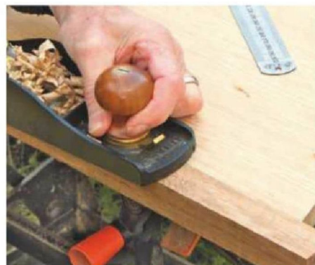
12 Plane lipping flush with the MDF surface. Use a cabinet scraper to finish, which will avoid damaging the veneer
