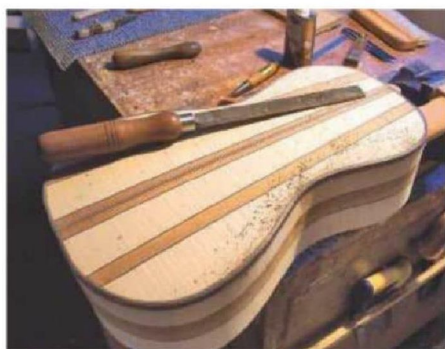
79 Cleaning up the bindings and purflings
