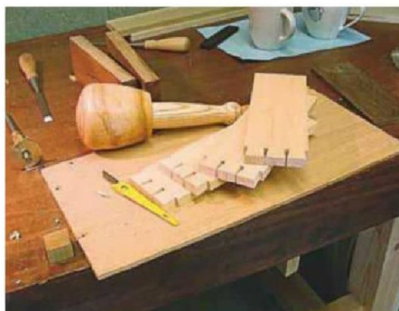
20 The rear dovetails were cut through but the front ones were lapped
