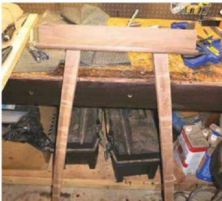
25 Test-fitting the outer tusks
