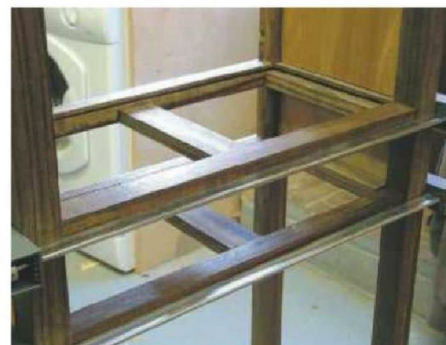
21 Note the grooves for the cabinet floor. The panel under the drawers was fitted from below
