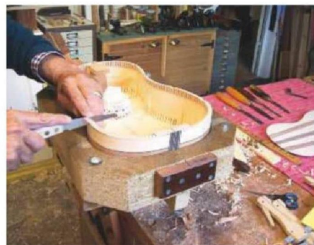
72 The razor saw is good for fine cuts
