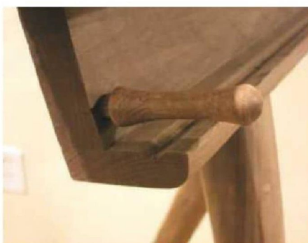
16 A guide for drilling dowel pegs will give a good placement near the edge
