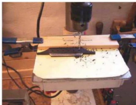
82 The bridge pin holes drilled
