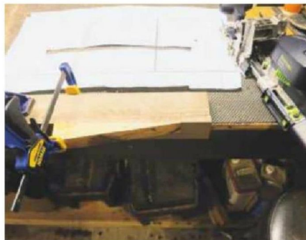
23 Homemade wedge to cut Dominos at an angle
