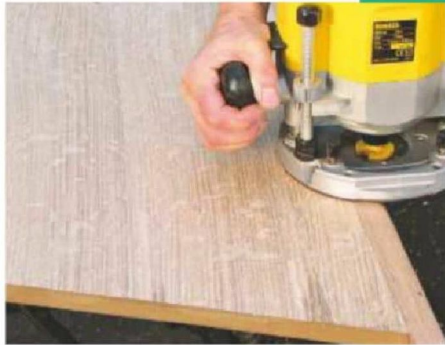
13 Saw to length, then rout the front edge with a bearing-guided rounding-over cutter. Complete with a plane
