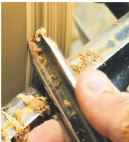
10 The close-up of the cutting edge shows the flute position; this optimum cutting angle will quickly remove wood, so be careful not to take stock away that you'll need
