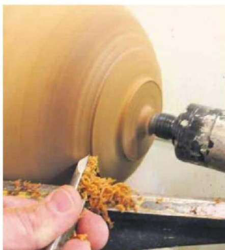
17 I'm going to use the new Axminster Evolution chuck so need a dovetail spigot; the bottom curve can be refined and the spigot turned with the Signature gouge
