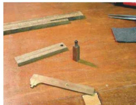
23 The ball catches were made from ovankol, using a rubber band for an improvised spring!
