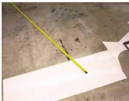
2 Using a tape measure as a beam compass
