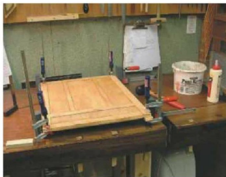
10 I used bridle joints to connect the rails and stiles, but you could just as easily use tenons
