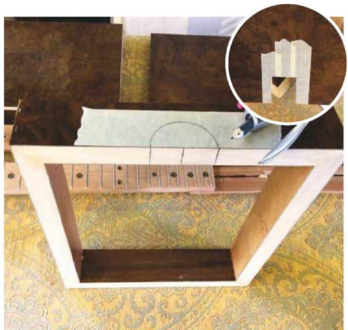
8 Using a compass, I marked out the semicircle for the neck and the rectangle to house the fret board. To protect the veneer, I used masking tape and a very fine jigsaw to cut the pieces out
