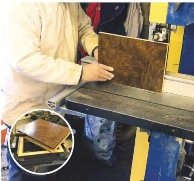
7 Using the tops and sides of the sideboard, I cut up the sections to form the boxes. Using a router, I cut a groove around the edges of the boxes so that only the veneer of the satin walnut would be seen when they were complete. The boxes were then mitred and glued using picture frame clamps
