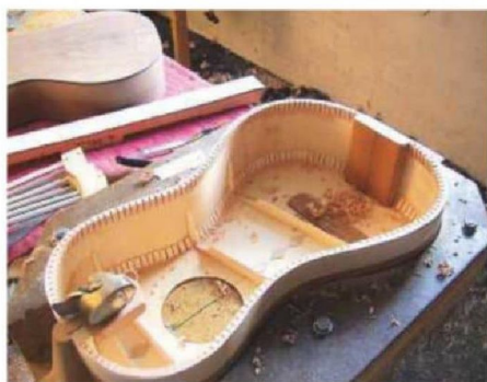
68 A thumb plane can be used to level the lining
