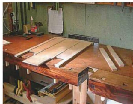
8 The panel components were laid out to find the best match of grain and colour
