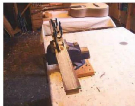
63 The back braces are curved on a sanding stick
