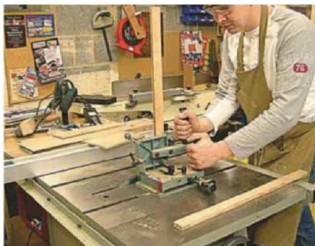
9 I cut the stub tenons on the back panel components, again using the sliding tenon carriage
