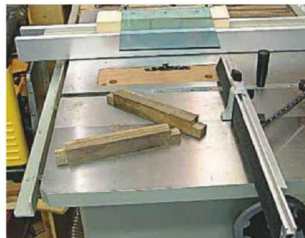
3 The tenons were cut on a table saw with a sliding carriage and an overhead guard
