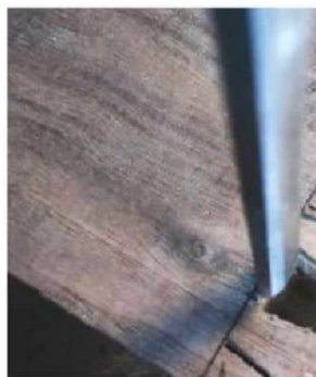
These can site in a knife line and chop through hardwood with ease, although the smallest chisel in this set will not do for daintier dovetails
