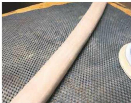
28 Sanding with a soft-pad random orbit sander using an 120-320 grit pad
