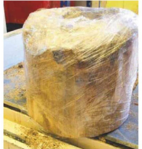
6 Because it's home time now, I protect the wood from splitting overnight by wrapping it in cling film/pallet wrap to stop the timber drying out
