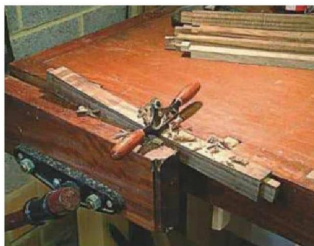
5 A spokeshave was used to cut the top rail from both ends, thus keeping tear-out to a minimum
