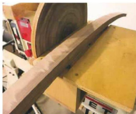
9 Breaking out the lathe-mounted disc sander
