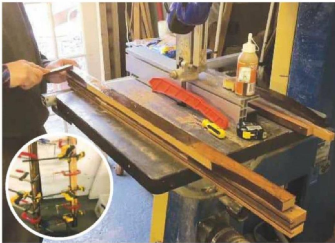
2 I then glued up the framework, which I think was mahogany due to the age of the sideboard and the fact a polyurethane glue was used
