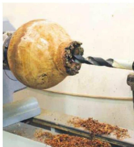
18 Whenever I hollow a pot like this one I drill the hole to the finished depth using a twist-type drill rather than a brad point or sawtooth bit to avoid a centre point
