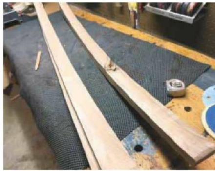
19 Using the legs as a straightedge
