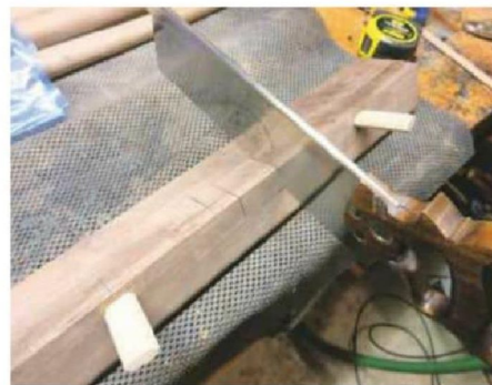
29 Cutting the notch for the centre tusk's pivot
