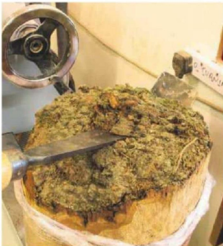
7 When working on an uneven project like this I like to mount the wood between centres, but first must clear the area away from the centre to achieve a positive drive off the wood, not the softer bark
