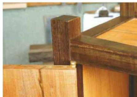
Hinges in place
