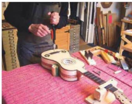
89 Drilling down through the bridge is a life shortening moment...
