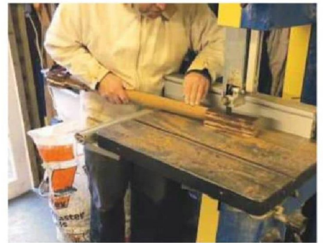
6 Shaping of the head of the guitar and heel then took place using the bandsaw
