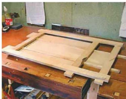
7 The back panel was made up of four panels, two stiles, three rails and two muntins
