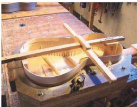
70 The jig that measures the curvature
