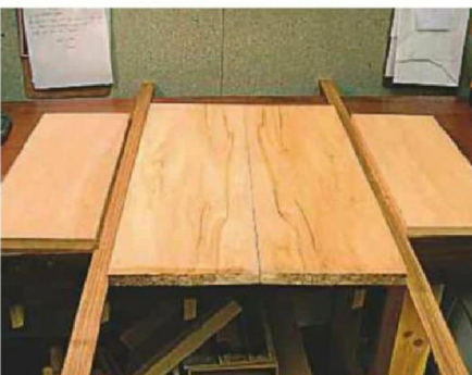
15 Make sure you take into account the overlapping rebates on the doors
