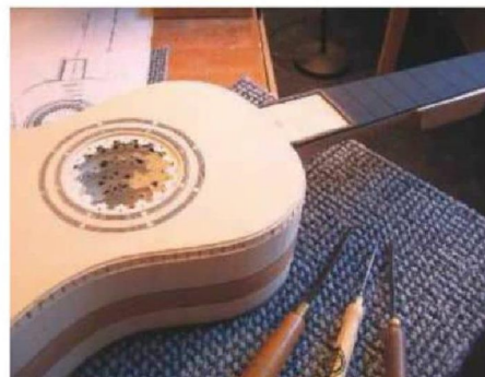
75 Rebates for the bindings and purflings applied to the front
