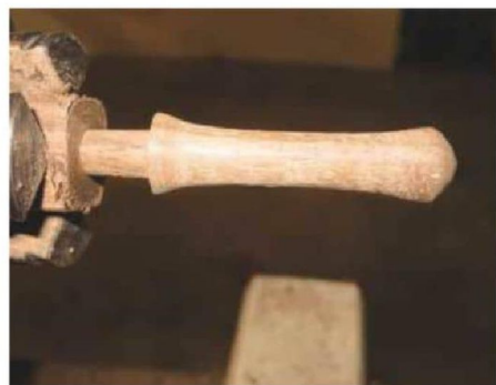
14 Mounted in a long-nose chuck
