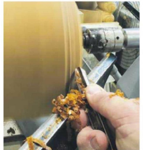
9 Start truing up the outside with the bowl gouge; I start by getting rid of some of the weight, especially as the lathe is being jumped about by the fact that the wood is so out of balance
