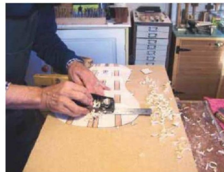
65 The back braces are gabled
