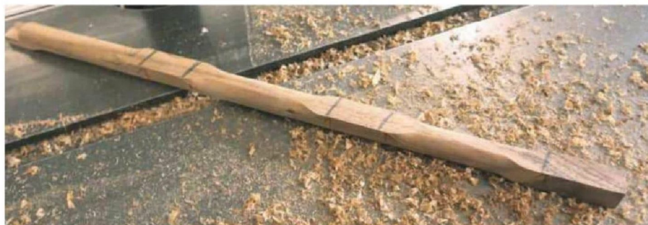
38 Rounding supports on the router table. I kept the joining areas square to aid in alignment later on. We will shape those by hand later
