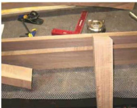
10 Here you can see how the ends have been mitred at 10°
