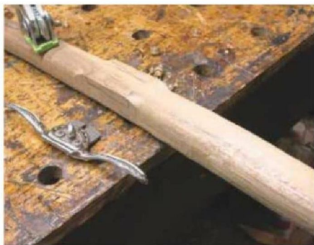
27 Using a spokeshave to blend the transitions
