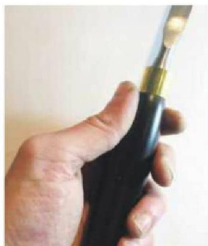
The stained beech handles are durable and attractive, although I found the rounded profile wasn't ideally suited for fine work with the smaller chisels
