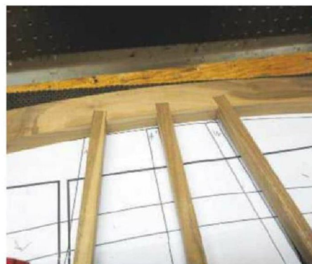
37 Test-fitting the supports
