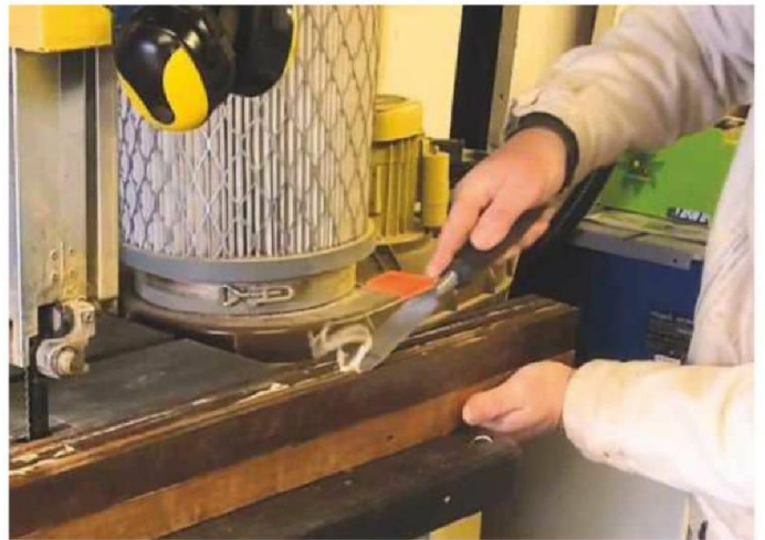
3 I paper-jointed the two sections together using PVA glue as I would need to split the necks once turned and then remove the excess polyurethane glue using a chisel
