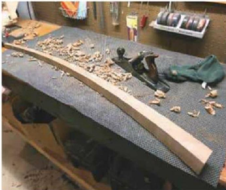
21 Using a jack plane to smooth out the sides
