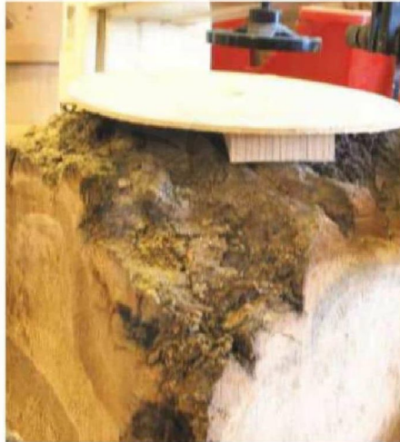
5 Before cutting around the disc on the bandsaw, I level the hardboard by putting some wooden spacers underneath to stop the board being forced down if it is touched with the blade
