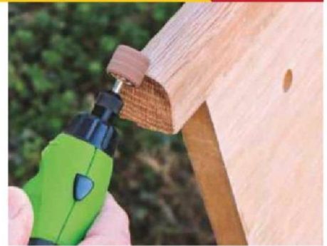
15 Round over ends of the lipping with a file, sanding block or mini-tool fitted with a drum sander
