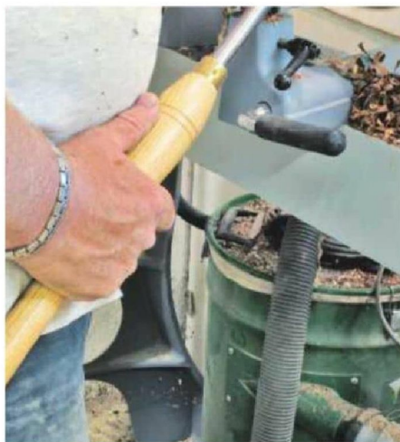
11 To counteract the forces being put on the gouge I've locked the handle into my hip; wherever possible I adopt this stance for greater control on the business end
