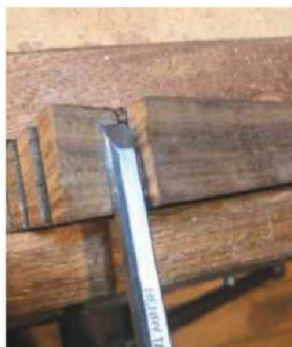
The blades are perfectly adept at cleaning up waste from dovetails, although I felt the handle shape was better suited to less intricate work
