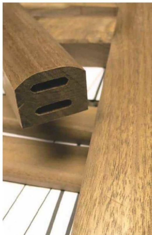
42 Close-up joint for the outside of the frame. Profile is the top half of a large roundover bit. Two small Dominos increase strength and improve alignment
