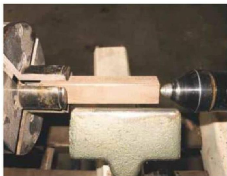
12 The peg blank mounted on the lathe
