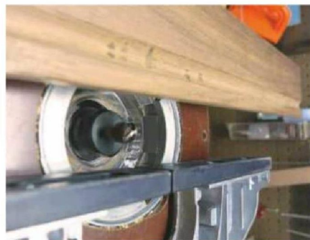
11 Use a bull-nose bit in a router table to cut the pencil slot
