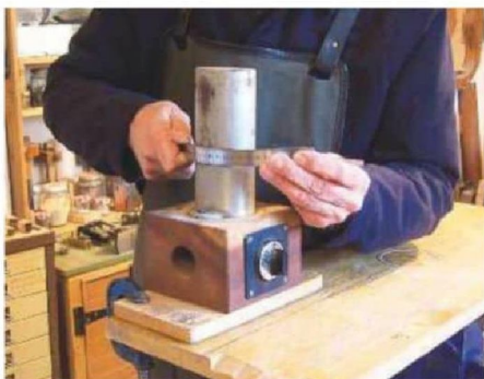
76 Bending the bindings on the hot iron
