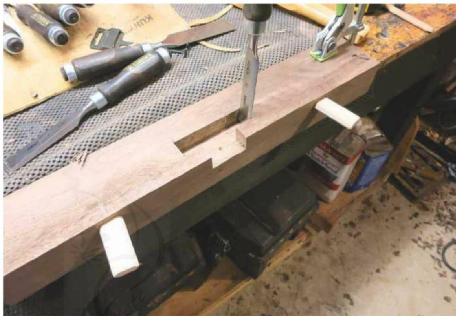
30 Completing the slot for the pivot with chisels in the corner
