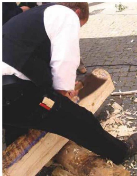
A German carpenter (Zimmerer) hewing a log into a beam. Note the blue chalk line snapped on the log to which the hewer works
