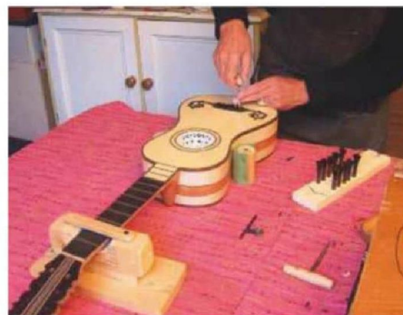
90 The bridge pin holes are reamed
