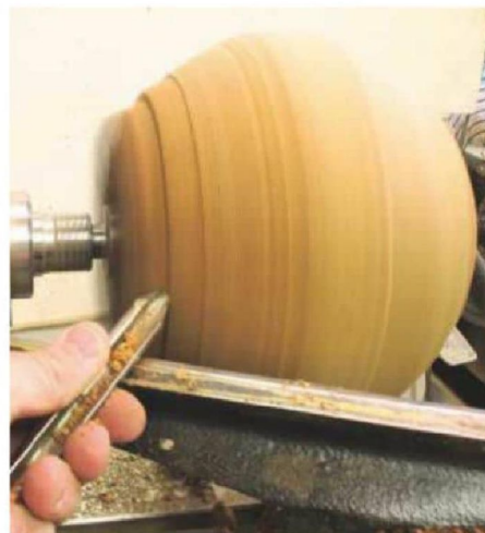
15 I like to get as much of the shape completed before mounting up on the chuck; even though this is technically against the grain, it's OK for the initial shaping of the piece
