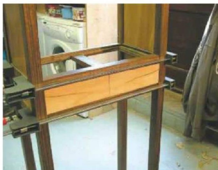
22 As the drawer fronts were cut from a single piece of sycamore, the grain runs true
