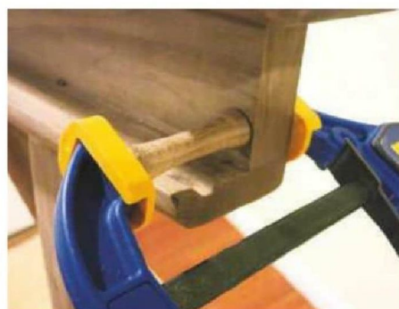
17 The peg glued and clamped into place
