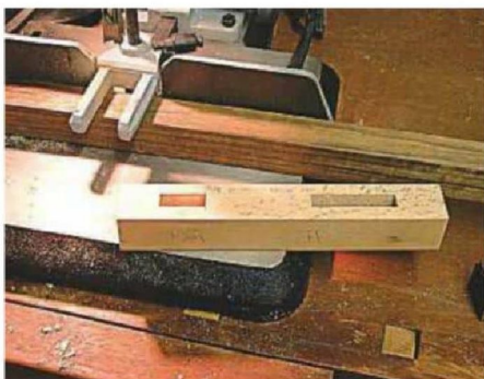
4 The mortises were cut with a mortiser, but can also be cut with a router or by hand
