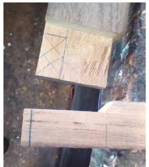
4 Haunched mortise & tenon marked out
