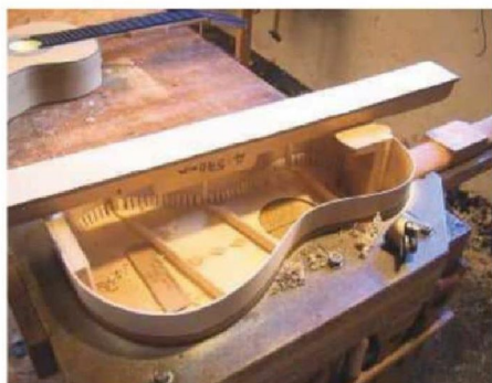
69 Curved sanding stick used to produce the 4mm lift
