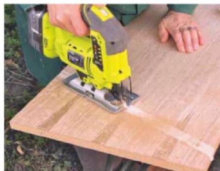
9 Cut MDF carefully with a jigsaw fitted with a fine-toothed blade. Tape will prevent the veneer from splintering
