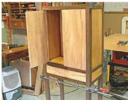
17 Now I could assemble it all – the carcass had to be assembled with the doors in place
