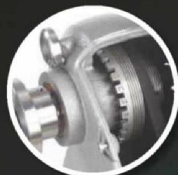
Heavy-duty spindle lock and 24 point indexing
