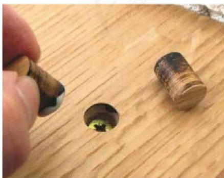
20 Cut matching plugs from solid oak. Brush on PVA glue and tap them firmly into holes
