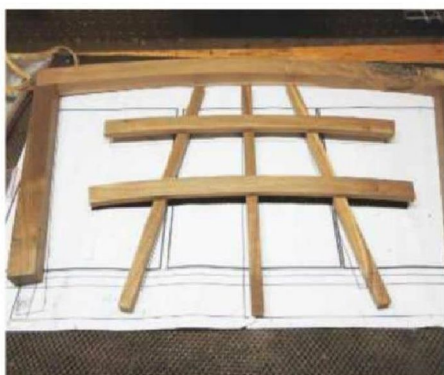
34 Laying out the top of the stand
