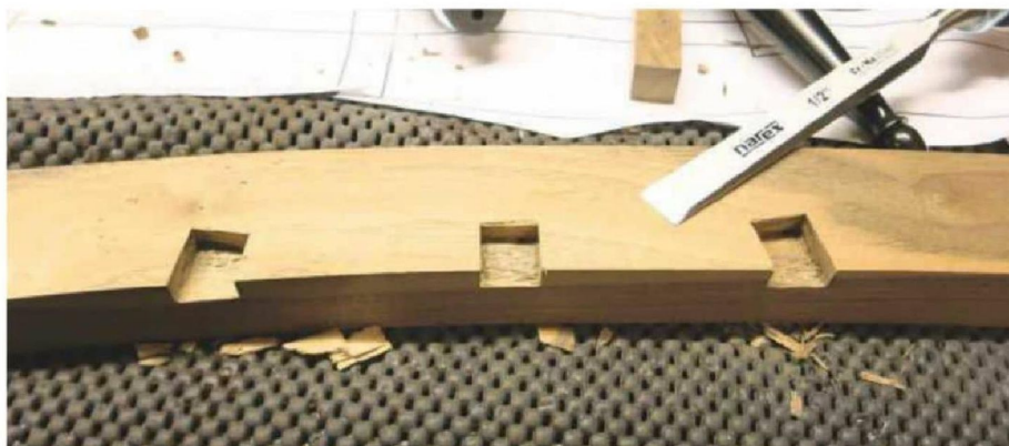
35 Chiselled lap joints to align music supports
