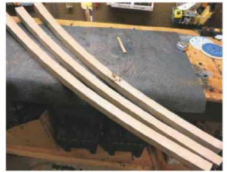
20 Tusks after tapering on the bandsaw
