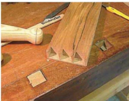
18 The dovetails on the drawer front were lapped, but watch out for the overlapping
