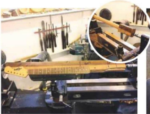
4 I placed the section between centres on the lathe, and as an additional means of security, put a 75mm screw in each square section at each end to make sure the material didn't separate with centrifugal force, as the two sections were paper-jointed. Once the turning was complete, it was basically a case of turning a spindle from square to round using a spindle roughing gouge
