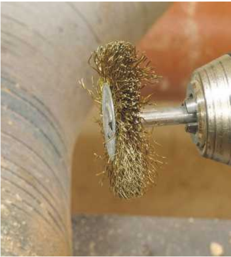
13 Initially I tried a steel brush mounted in the drill but found it a little harsh on the small bricks, so I changed to a brass one. I locked the spindle on the lathe so I could apply enough pressure to brush the grain out
