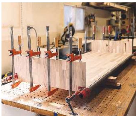
14 F-clamps help to hold the two sides of the corner together while the glue dries
