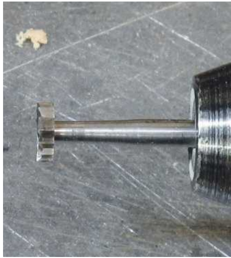
11 This is a tiny 2mm-wide slotting saw that I bought from an engineering show many years ago. It's used at about 20,000rpm in a Proxxon mini drill
