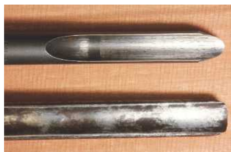
9 Ladyfinger (top) and fingernail (bottom) detail gouge noses
