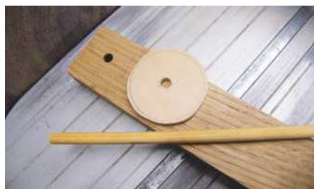
1 The discs are cut a little oversize to begin with
