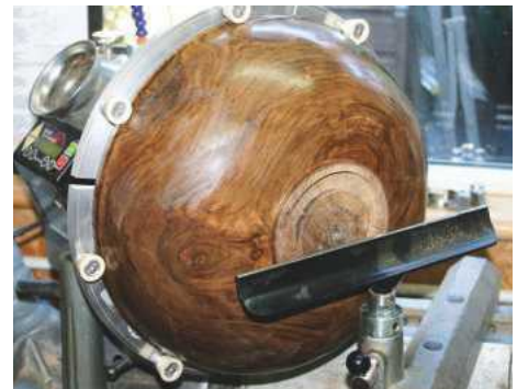
27 The bowl has been reversed and is securely held in some Axminster 400mm button jaws to enable the final removal of the spigot and to refine the base of the bowl. The rubber buttons on the outermost screw holes on the jaws just exceeded the 406mm swing limit of the lathe so the headstock was swivelled out by an angle of 22.5°. For safety reasons, I never use button jaws at a lathe rotation speed in excess of 600rpm
