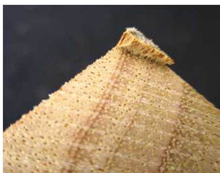
Don't forget to press down at the end of the cut!
