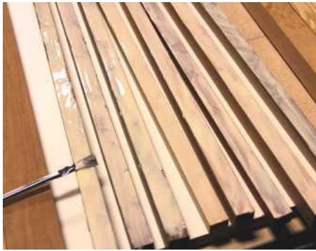
6 Separating your cutting board strips into two groups, no wider than the maximum capacity of your planer, glue the strips together
