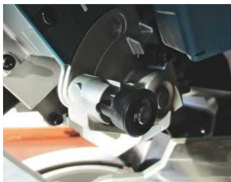
Lock pin secured for free movement
