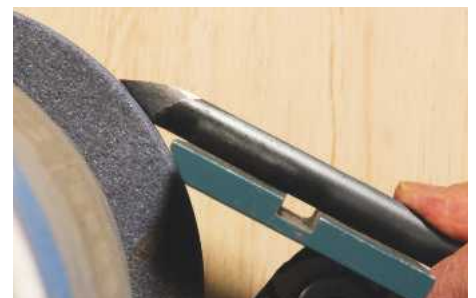
10 Grinding the left-hand bevel of a ladyfinger nose on a detail gouge. The gouge will be slowly rotated anti-clockwise while the tool is thrust slowly forward
