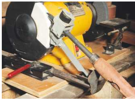
5 Grinding a detail gouge with a pivoting jig, here with the minimum positive knee angle
