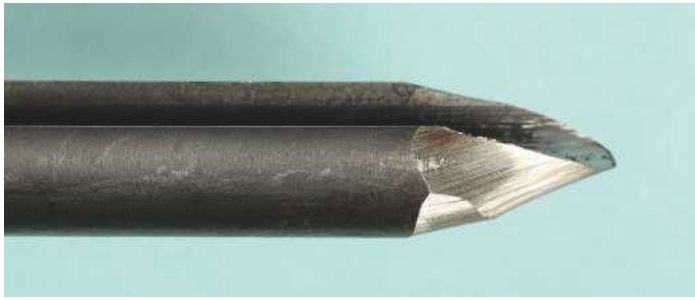
12 A detail gouge with a double bevel
