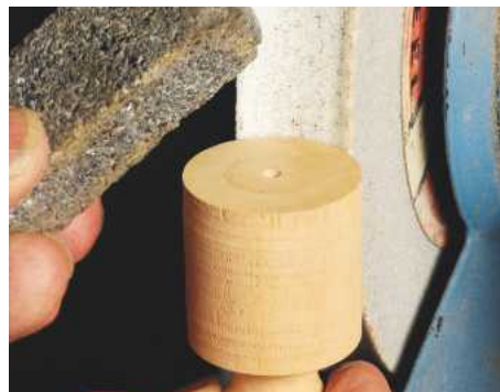
15 Using a coarse aluminium oxide dressing stick to grind a concave periphery in an aluminium oxide grinding wheel. The 17mm wooden reference radius is the smallest radius surface which a gouge ground on this wheel can cut without bevel-heel crushing
