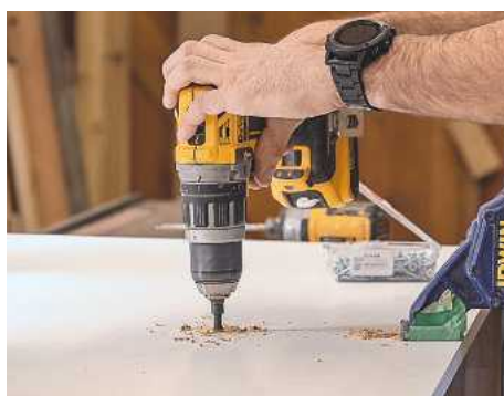
23 Countersinking a series of screw holes and securing the drawer bottom in place
