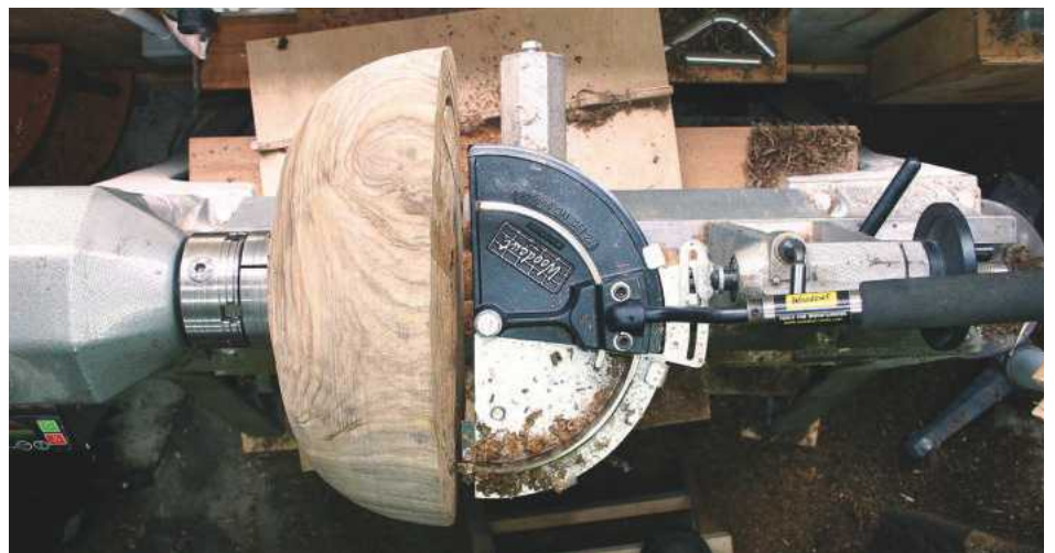
11 This top view of the Bowl Saver shows the setup very clearly. All set to start taking the first 'daughter' core from the 'Walnut Whopper' using the larger 130mm radius cutting blade. A low lathe speed of between 400-600rpm is used for this process
