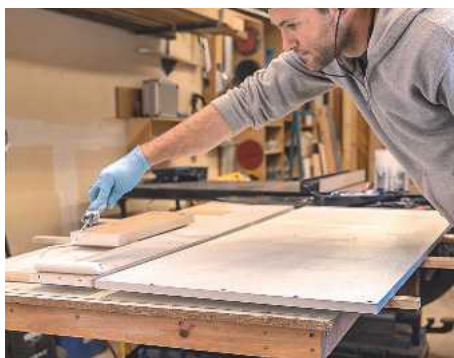
17 Applying a custom semi-gloss paint to the bottom of the desk
