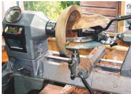
15 Birth of the 'granddaughter' bowl cut from the 'daughter' bowl using the Bowl Saver with the smaller blade of 100mm radius
