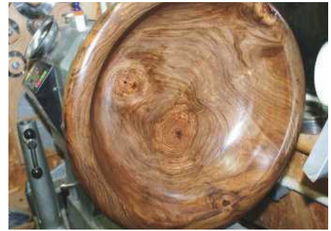
26 The rim and inside of the bowl after completion. The wood was finally prepared by a combination of power and hand sanding – cloth-backed abrasive grit sizes were 80, 100, 120, 150, 180, 220, 240, 280, 320, 400, 500 and 600. To clean the surface and get some idea of the finished appearance, white spirit was applied to the wood using some kitchen roll. This emphasised the spectacular figuring of the wood, especially in the vicinity of the two pith areas
