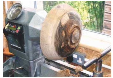
14 A spigot (within the decorative plinth) was created on the base of the 'daughter' bowl to enable another 'granddaughter' core to be cut out using the Bowl Saver
