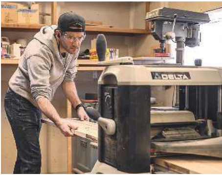
7 Using the planer to carry out multiple passes
