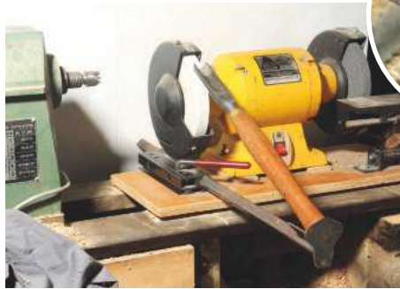
2 Grinding a spindle roughing gouge on a Wolverine handle-end jig
