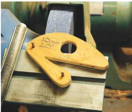
7 A Darlow template for a detail gouge 19mm wide with a 25° sharpening angle. Made quickly and easily from the diagrams provided free on the website – www.mikedarlow.com – these computer-designed templates compensate for grinding wheel wear
