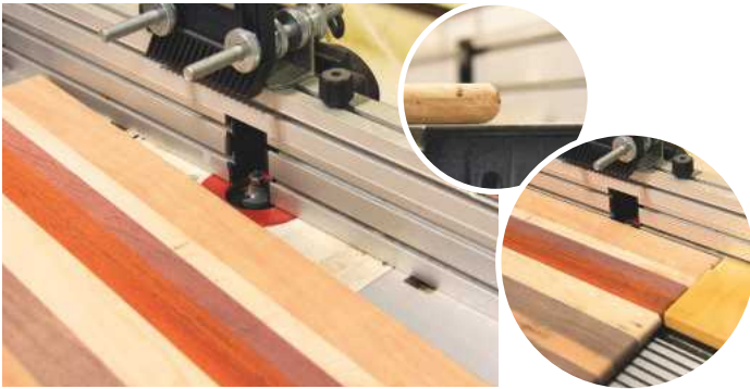
10 Round over the top and bottom edges with a roundover bit fitted in the router table
