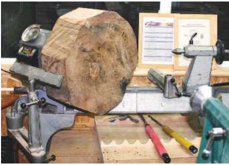
5 The wood was too big for the 406mm swing of my Nova DVR lathe, so the headstock was swivelled by 22° and the toolrest outrigger used
