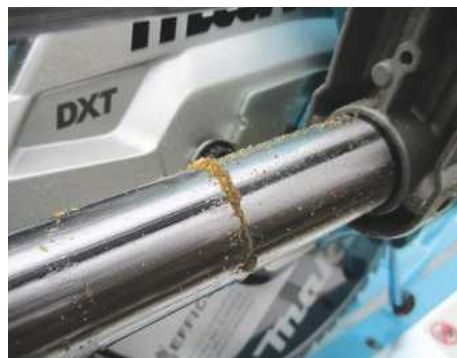
Well-greased components soon trap the dust
