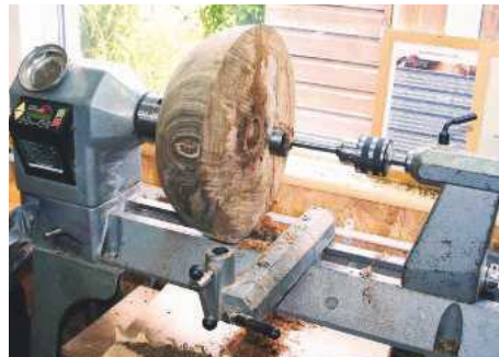
9 A 12mm deep recess was drilled in the top surface of the bowl with a pilot Forstner bit of 38mm diameter followed by a bit of 60mm diameter. This would subsequently be used to attach the 'daughter' bowls to the lathe by means of 50mm chuck jaws expanding into the recess
