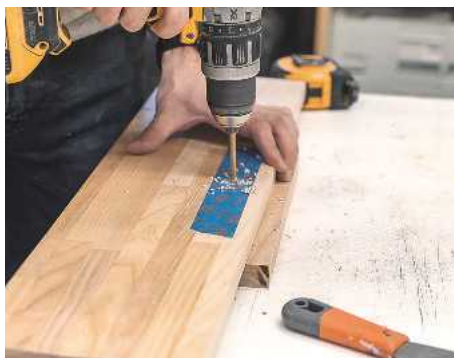
25 Using a piece of painter's tape when drilling the holes for the drawer pulls
