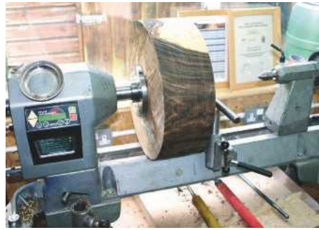
6 The wood after truing up. The slight reduction in diameter enabled the headstock to be swung back into its normal position with the axis parallel with the lathe bed bars. The superb figuring of the walnut was now becoming apparent
