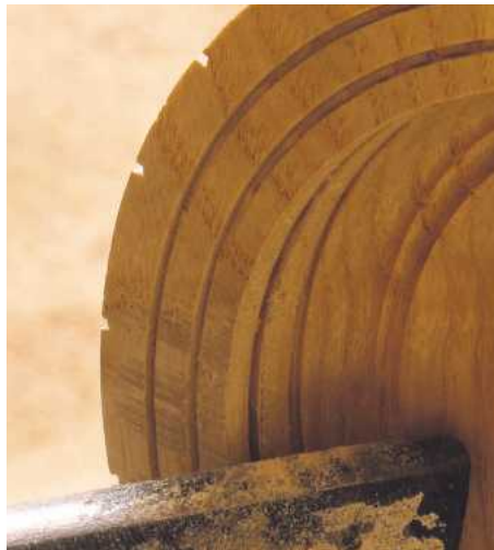
17 Here you can see the position of the toolrest. I have now sanded the edge and am only taking two rows of bricks into the bowl; if it were larger I may have gone for three
