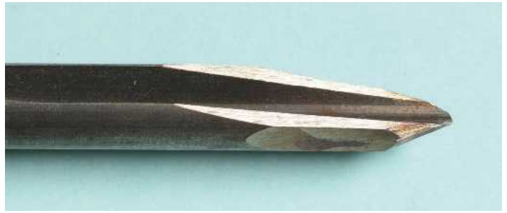
13 A small detail gouge nose ground on a bowl gouge
