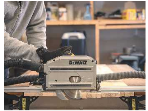
9 Using the track saw to square up the ends of the desk top
