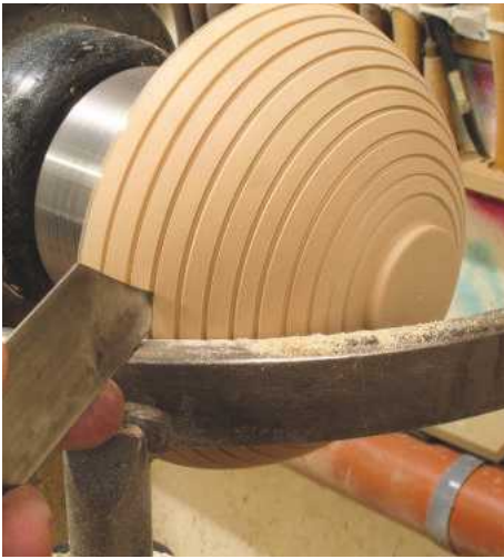
10 The 2mm parting tool is just the right size to cut the circular slots in the bowl. I went about 2mm deep all the way around and, as you can see, they get a little closer towards the base
