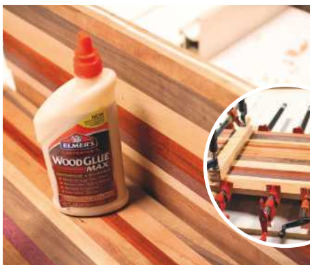
8 Glue the two boards together and clamp up overnight using cauls to keep everything aligned
