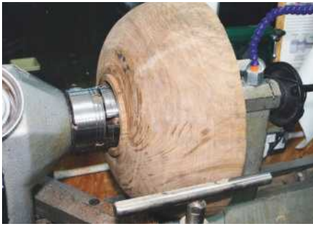
24 After successfully truing up the distorted dovetailed spigot, this photo shows the bowl reversed and securely mounted on the lathe, gripped by the chuck jaws
