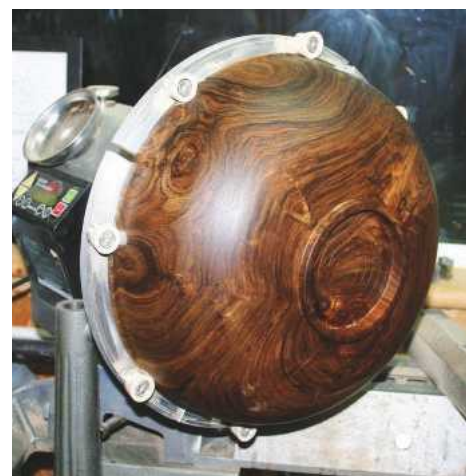
29 The completed base of the bowl with the spigot removed and the area within the plinth decorated with some beading rings, which are incised using the point of a skew chisel
