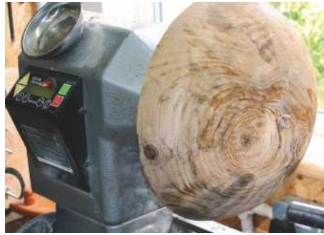
13 The 'daughter' bowl mounted on the lathe by means of the 50mm chuck jaws expanded into the 60mm recess previously drilled (see photo 9 ). This enabled a spigot to be created ( photo 14 )
