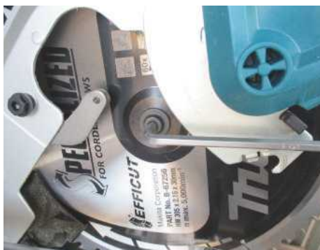
Access to blade removal requires guard to be moved
