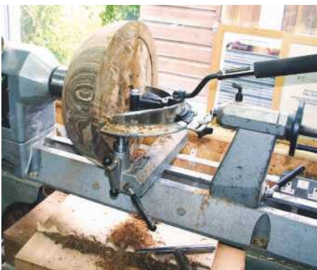
10 The Bowl Saver is attached to the lathe by means of the banjo (toolrest holder) with additional support from the Morse taper of the tailstock. After careful setting up, the core is cut by slowly swinging the black handle round in a clockwise direction so that the stellite-tipped end of the curved cutting blade cuts out the core in the spinning wood
