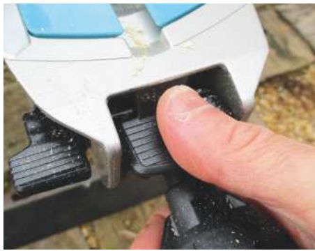
Index unlocking at the press of a thumb
