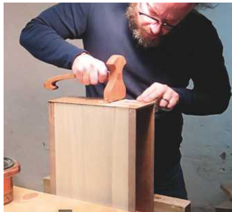
Hammer veneering the drawer box carcass with thick lacewood veneer
