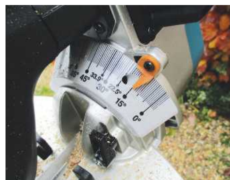
Easy to read, accurate carriage tilt gauge for bevels
