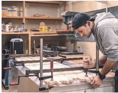
8 Clamping the desk top to my flat worktable
