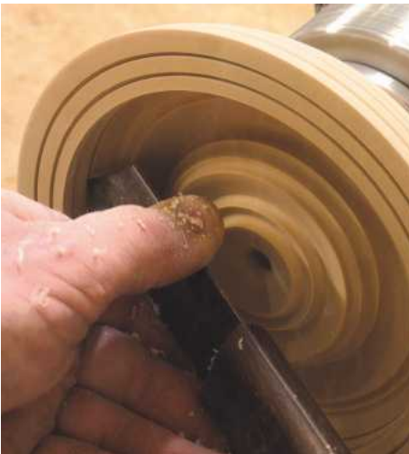
16 The small parting tool cuts the grooves on the inside. The edge of the bowl is quite sharp at this stage so be careful not to cut yourself
