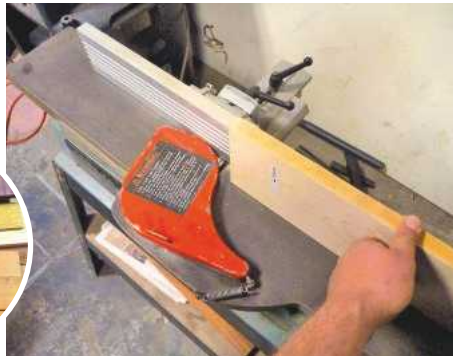
2 Use a jointer to prepare one edge; this creates a straight edge, which you can use later to push against the table saw fence to make a straight cut
