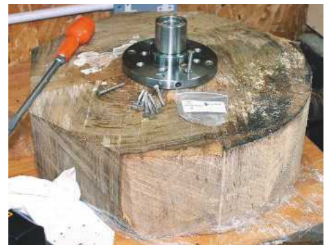
4 I decided to mount the blank on the lathe by screwing it to a 150mm faceplate with 12 x No.14 size 38mm wood screws
