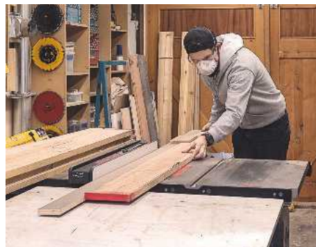
2 Using the table saw to rip pieces of 4 × 4 maple and ash into 25mm wide strips
