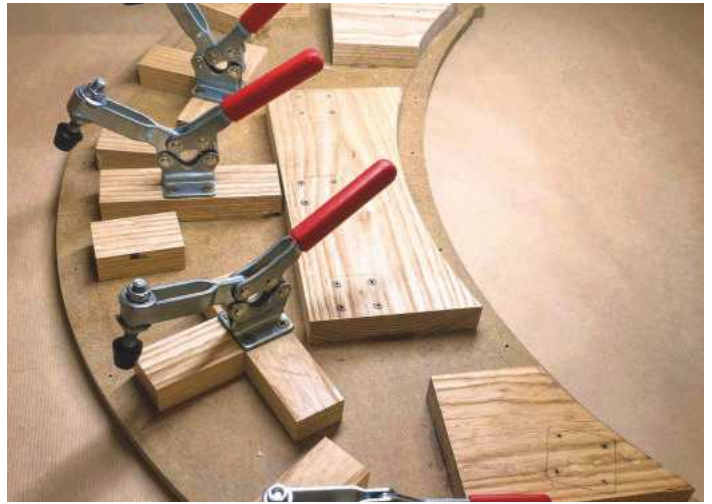
One of several custom jigs built to make the tables
