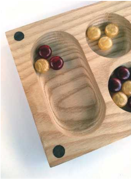
3 Two of the black walnut cross-grained plugs, which contrast with the ash. Underneath each sits a rare-earth magnet
