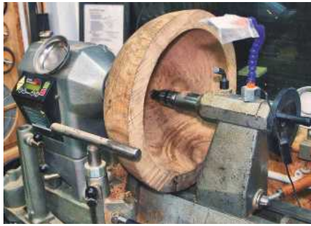
25 With the revolving Steb centre still in place to provide additional tailstock support, the rim and top part of the outside were trued up and turned to their final design. The tailstock was then removed to allow the interior and bottom of the bowl to be completed
