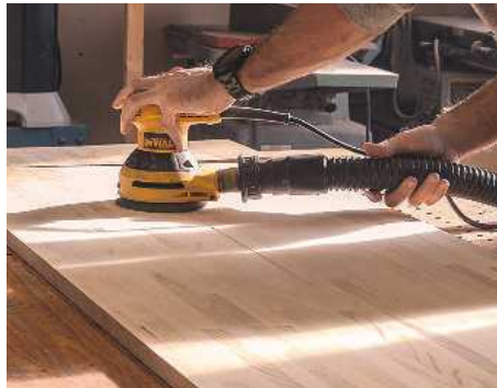
11 Sanding the desk top using a random orbital sander
