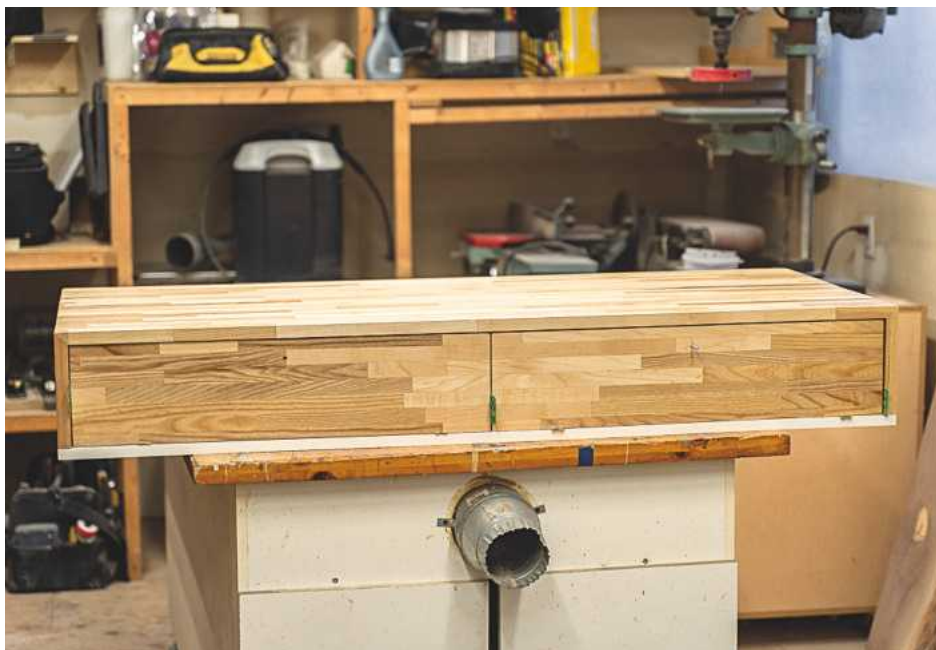
27 The 3mm plastic shims I used to position the drawer fronts in the mouth of the desk
