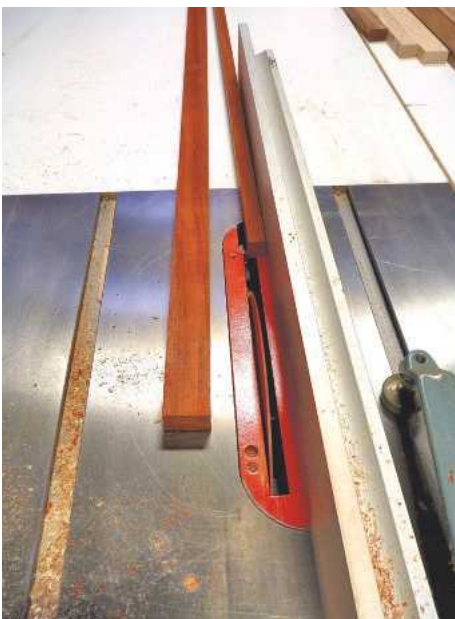
4 Placing the previously jointed edge against the fence, cut strips of random width
