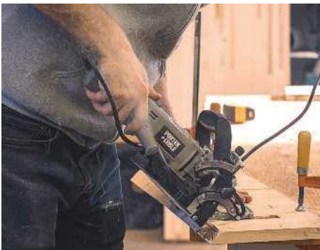
12 A biscuit jointer is used to help secure the 90° 'waterfall' corners
