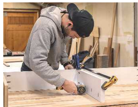
18 To attach the MDF back and centre drawer mounts to the desk top, I used a series of pocket screws
