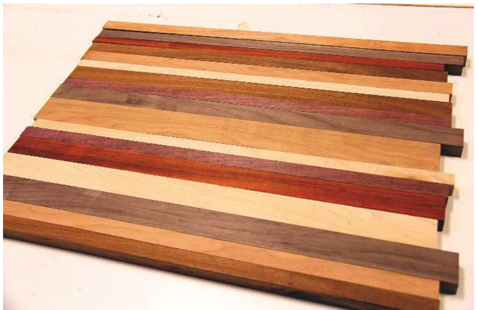
5 Once the strips are all cut, arrange them according to your tastes
