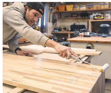
15 Applying a protective clear coat to the desk top
