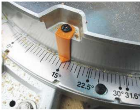
Settings for most of the common mitre angles are indexed
