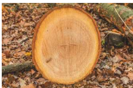
Cross-section tree trunk of American oak, with heartwood, sapwood, bark, and clearly visible marrow rays
