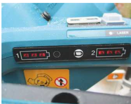
Easy to read indicators inside the hand grip show battery condition
