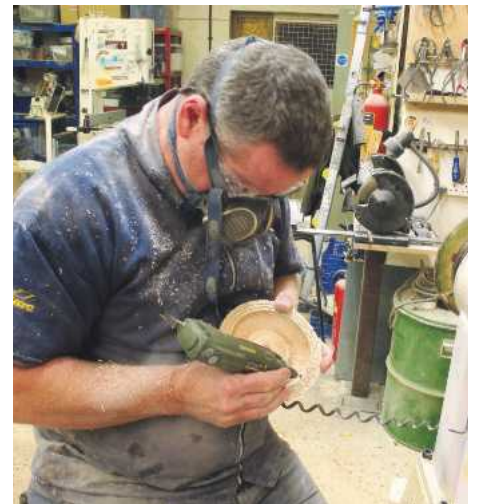
18 To make the vertical grooves I found it much easier to take the bowl off the lathe and sit down. I find the eclipse dust mask more comfortable than the full-blooded respirator for this type of light work
