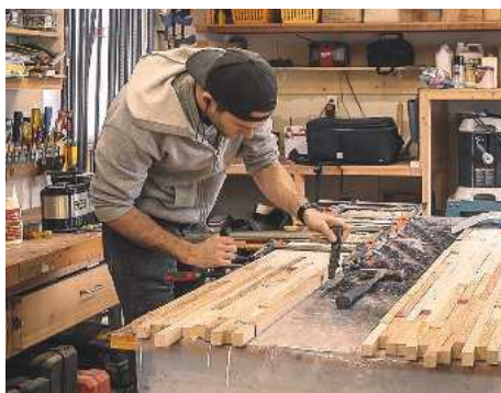
6 Using a series of F-clamps to clamp everything together
