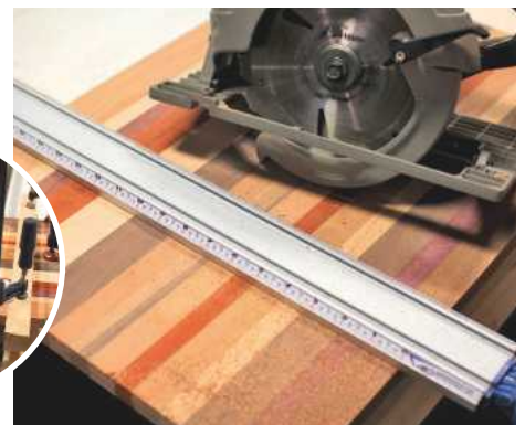
9 Alternatively, you can use a circular saw and straightedge, instead of a sliding mitre saw, to cut off the uneven edge
