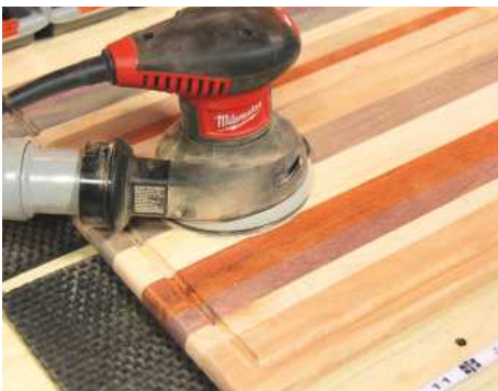
12 Sand the board using a random orbital palm sander and work through the grits
