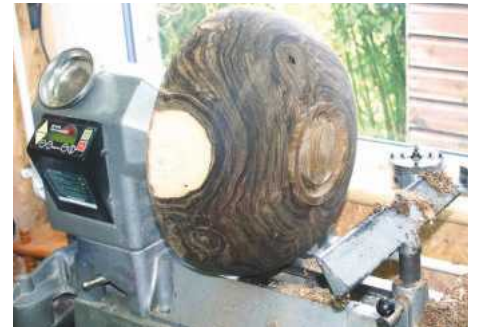
7 The exterior of the bowl after rough turning revealed two complex pith areas indicating that the slice had been taken near the base of a fork or crotch. An 80mm diameter 15° dovetail spigot has been cut on the base together with a rough decorative plinth
