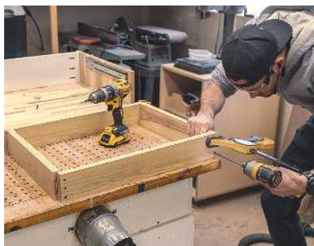
20 Screwing one of the drawer frames together
