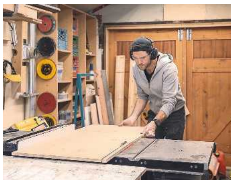
16 Using the table saw to cut the 20mm sheet of MDF into two pieces
