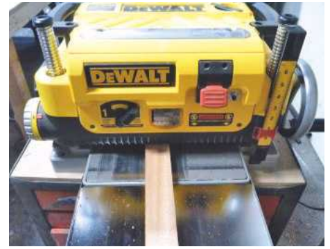
3 Take the already dimensioned face and place it face down onto your planer bed, then run the piece of wood through the planer
