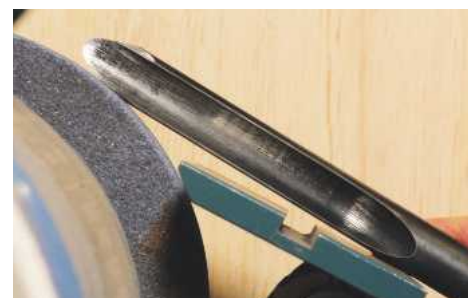
11 Completing the grinding of the left-hand bevel. Do not thrust the gouge more forward than necessary, or the radial sharpening angles are further reduced
