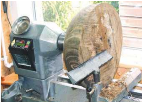
8 The bowl has been reversed on the lathe and is held securely by the chuck jaws gripping the spigot. The faceplate has been removed and there is now a choice of either using gouges to hollow out the bowl or else to core the inside with a specialist tool to enable several smaller bowls to be made from what would otherwise be wasted as a mass of shavings! I opted to use my Woodcut Bowl Saver coring system to make two successive cores
