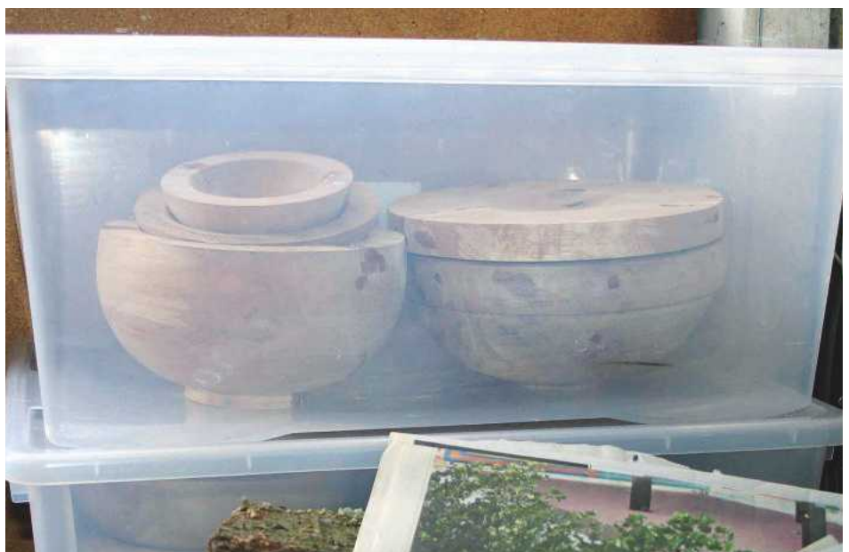
18 Green turnings quarantined in a lidded plastic box. This effectively prevents the turnings from losing moisture through evaporation
