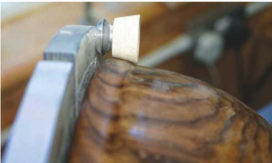
28 Close-up showing how the Axminster conical rubber buttons gently but firmly hold the bowl rim securely to the button jaws. In this instance they have been used with Axminster Stacking Turn Studs to increase their holding depth. These studs with a sharp ridge are designed to be used with the button jaws to directly grip wood but they have a good secondary use here to increase the holding depth of the rubber buttons. It is also worth noting that the Axminster rubber buttons are very well designed in their conical shape and with metal inserts to protect the rubber from damage from holding the machine screws. This is in contrast with some other makes of these jaws where the button design is very poor. The good news is that the Axminster buttons can be purchased separately and are secured with M6 machine screws, which make them compatible with most common makes of this jaw type
