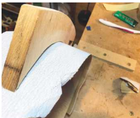
I used a piece of flexibly as a backing for sandpaper to sand the curved areas
