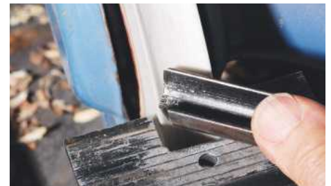
16 Grinding a convex bevel by axially rotating the gouge. The steeper the gouge's presentation, the less convex the bevel
