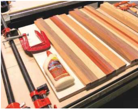
6 Separating your cutting board strips into two groups, no wider than the maximum capacity of your planer, glue the strips together
