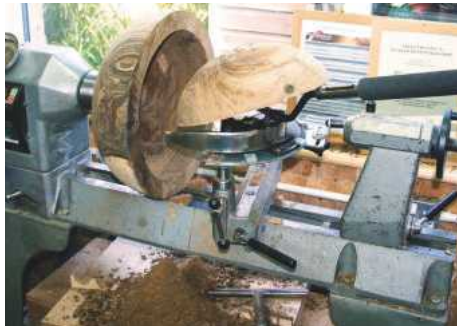
12 Birth of the 'daughter' bowl cut using the large Bowl Saver blade of 130mm radius
