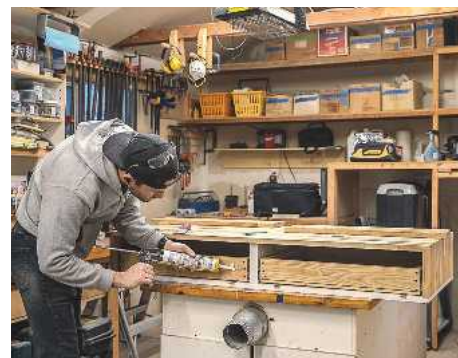
26 'No More Nails' is a great help when it comes to installing the drawer fronts
