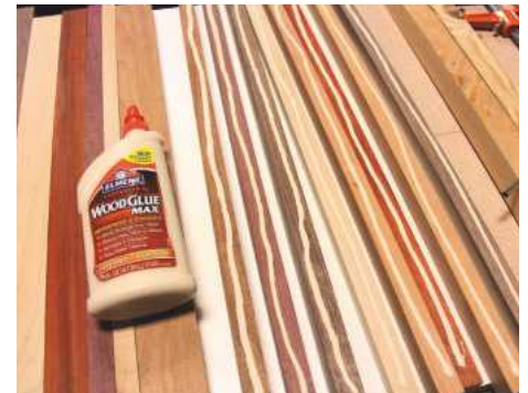
6 Separating your cutting board strips into two groups, no wider than the maximum capacity of your planer, glue the strips together
