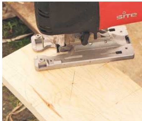
11 Cut around curve with a jigsaw fitted with a narrow blade, keeping to the waste side of the line
