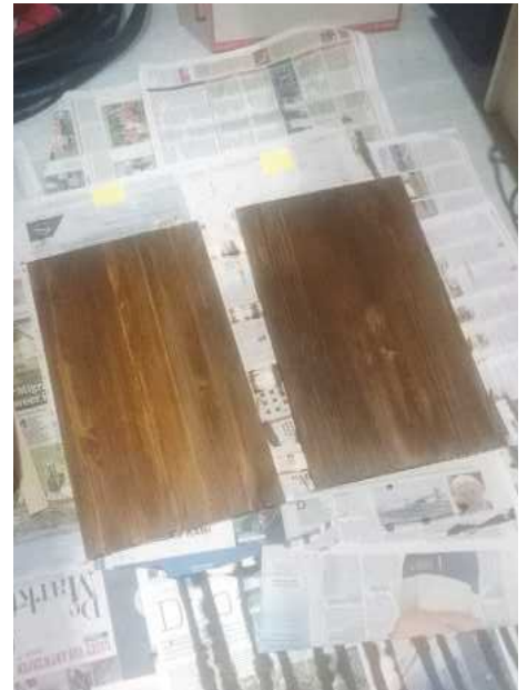
53 First stain the outside of all side panels in walnut (in just one layer)
