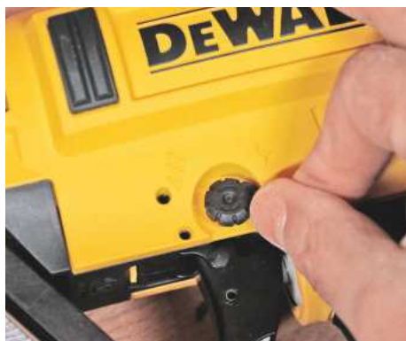
Bump and sequential firing is set with this dial
