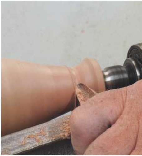
19 I can now create the fish tail shape on the top by cutting a cove from the right; this needs to blend seamlessly into the curve on the left. Imagine the top curve ending at a point on the bottom
