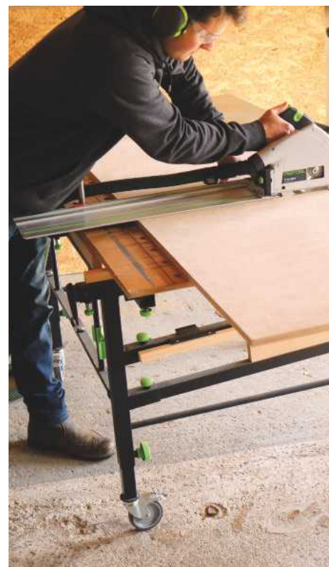
Using the STM 1800 as a cutting station when fitted with a Festool TS55 plunge saw and guide rail
