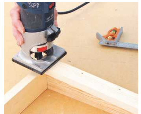
15 Sand arries on shelves, then shape the ends of the support battens with a bearing-guided roundover router bit
