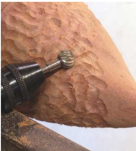
25 Any small rotary burr can be used for the texturing; the one I'm using here happens to be the ball cutter of a tool called the Decorating Elf from Henry Taylor Tools. I have found it to cut really cleanly on most timbers
