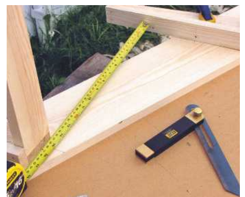
18 Screw upper and lower shelves to uprights first, then check the position of the middle shelf
