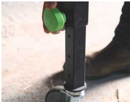
Quick-release auto-locating leg height adjustment is possible
