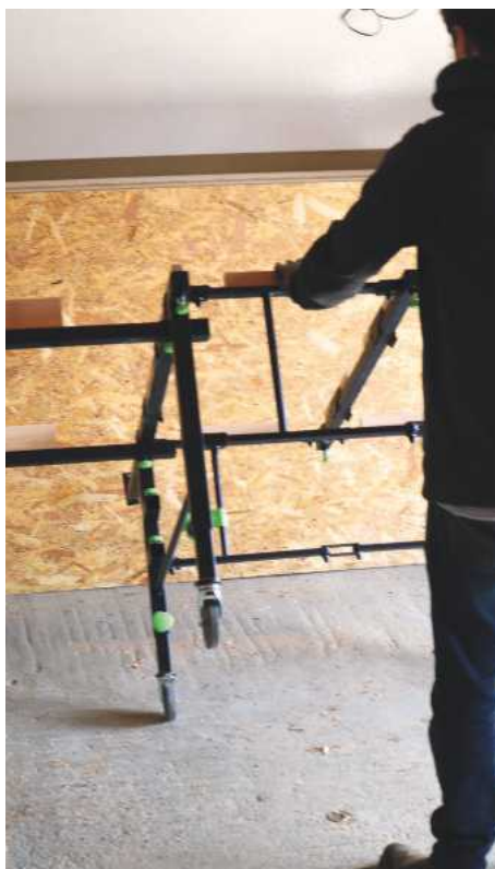
The STM 1800 tilts on its two locking wheels
