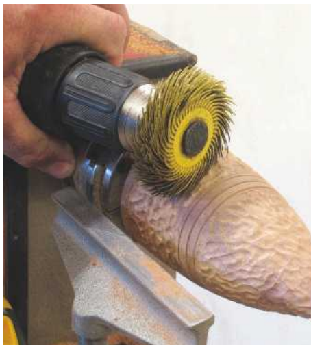
26 Any fibres that are picked up by the cutter can be cleaned off using a rotary sanding brush. This 3M sanding wheel is soft enough not to remove the texture
