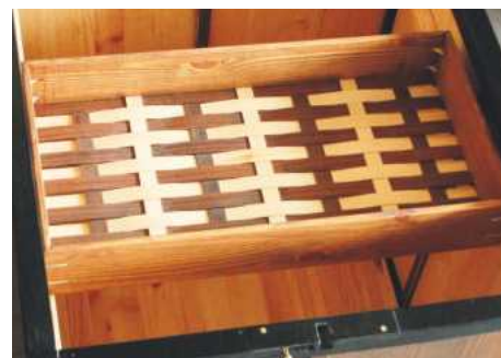
42 The blanket chest also features a sliding, removable compartment, which rests on top of two wooden rails that can be mounted in the frame
