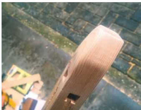
41 Use abrasives to reach the curve drawn on the bottom of each leg
