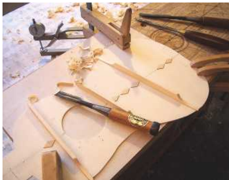
46 The bars are scalloped at either end
