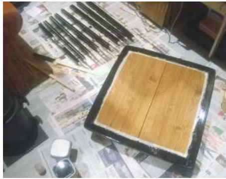
58 As with the frame, prime and paint the border black (on both the bottom and top side of the lid)
