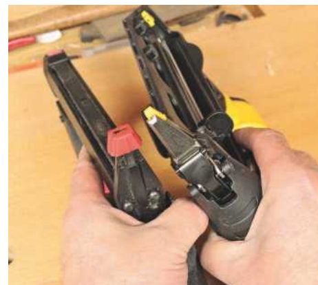
The DeWalt nose (right) is minuscule in comparison to a standard-nosed gun
