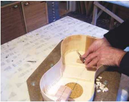
50 Tentellones are put into place with tweezers
