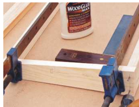
6 Spread glue and cramp shelf components together, leaving the ends slightly proud; punch heads below the surface
