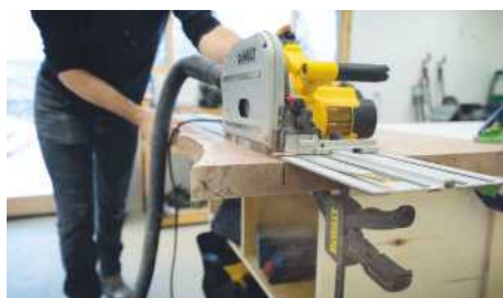
4 I also used the track saw to square up the ends of the slab
