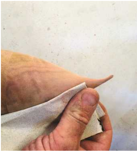
22 Once you have removed the timber you don't want, the point on the end needs sanding. As I am going to texture the box, I only sand with 150 grit, but if you wanted a natural finish, then you need to go through the grits
