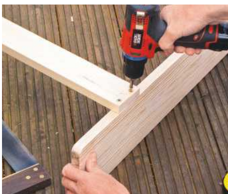
23 Add a stretcher rail across rear uprights for rigidity and strength; fix in place with 5mm screws
