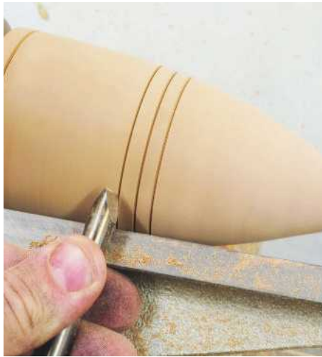
23 Use the skew to cut some small grooves; this offers some parameters for you to texture between. I also cut a groove on the joint of the box to hide the fact that the grain probably doesn't line up now
