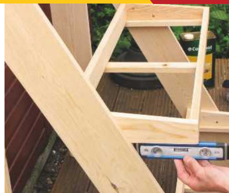
21 To check the length of the rear upright, cramp together and adjust until all shelves are level
