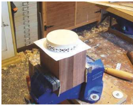
57 The first layer is glued up
