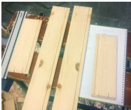
48 To strengthen the mitre joints, I cut two slots in each corner
