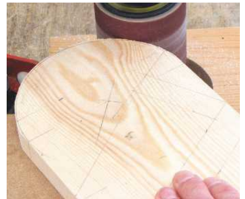
12 Clean up curved ends on a sanding drum mounted in a drillstand; cut rear uprights in the same way
