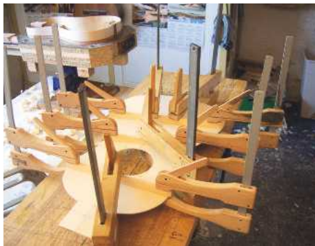
45 The harmonic bars are clamped into place
