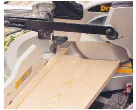
9 Set the mitre saw to 27° and cut the lower end of the front uprights – round off any sharp corners
