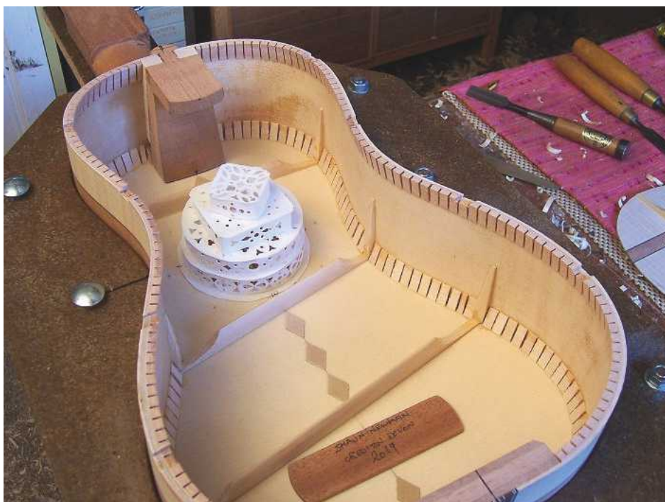
61 The completed rose is fitted
