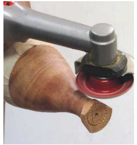
21 The shaping can be done using a rasp, Microplane or in my case, a powered rotary rasp. The Proxxon mini angle grinder with the carbide disc is user-friendly and perfect for small projects such as this
