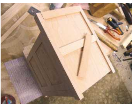
11 Applying the case rails
