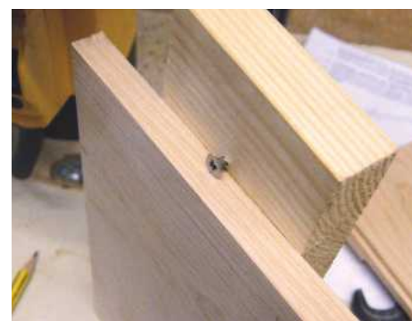
2 Scoring the edge of the wood prior to routing the rebate
