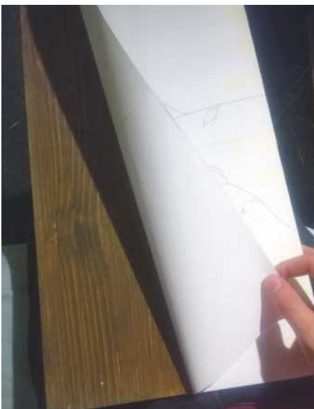
63 To carve the design into each panel, use several pieces of masking tape to attach the sheet of paper onto only one side of a panel
