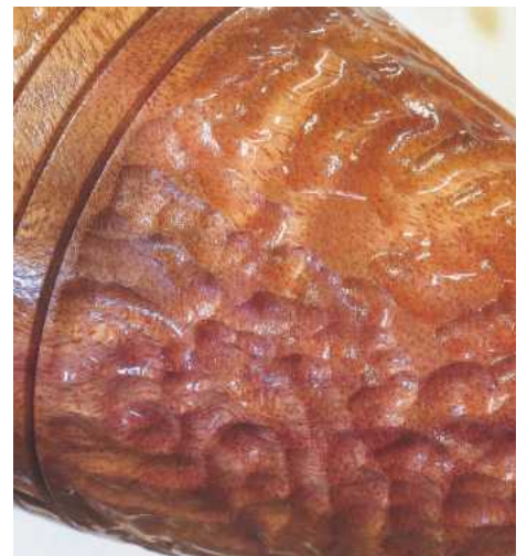
27 It's always worth giving the textured surface a coat of sanding sealer; this will make any loose fibres stand up so you can sand them off. This is the first time you can see what the wood will look like when it's finished
