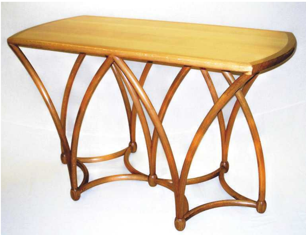
13 The completed table was finished using thinned linseed oil, Danish oil and finishing oil
