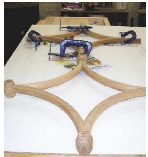
11 Bottom rails being checked against the rod before being glued together
