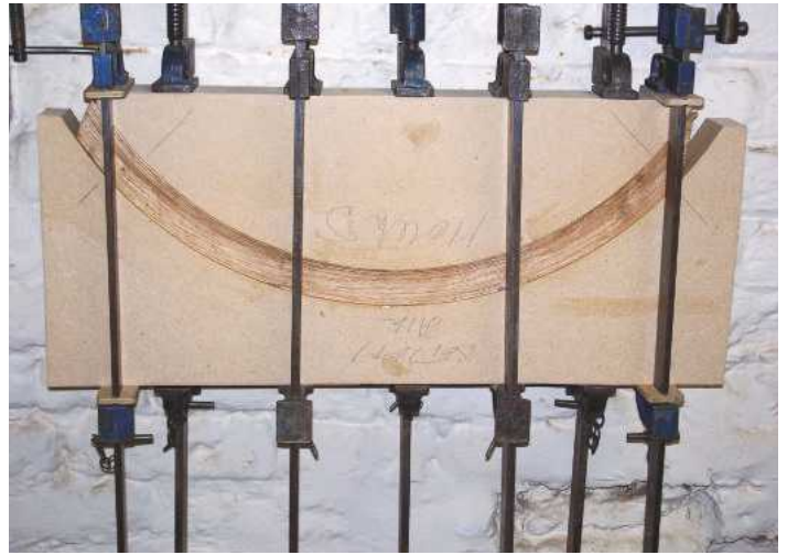
9 Bottom rail glued up in mould
