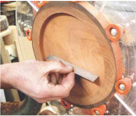
3 Use a small straightedge to check the flatness of the surface
