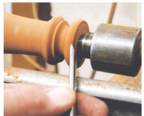
18 Use the long point of the skew to clean up both ends
