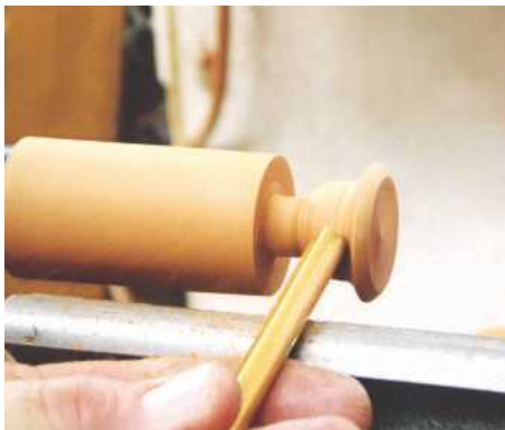
14 Turn the feet carefully; check with Vernier callipers that they're all the same
