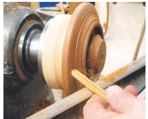
10 Use the 6mm gouge and the parting tool to turn the rest of the base
