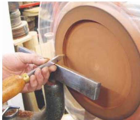
2 Use the parting tool to turn the edge; take a slow cut to ensure a good finish
