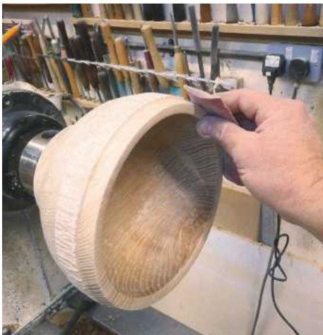
22 The top rim needs to be sanded before the back of the bowl is worked on, as you'll not be able to access it when the bowl is remounted on the button jaws
