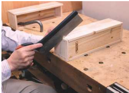
18 Elevate the work so you can saw the kerfs in a sitting position, without bending and getting tired
