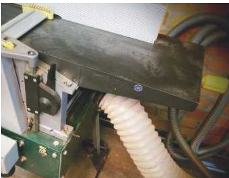
7 On my surface planer, the cutter rotation throws the chippings directly into the chute for the extractor to catch and suck away. Full marks to Record
