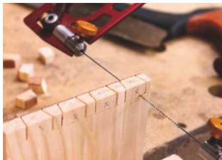
10 Install the fret saw's blade with the teeth pointing at the handle so it cuts on the pull strokes
