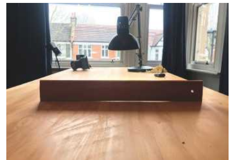
The straightedge doesn't lie – a valley runs through this table top
