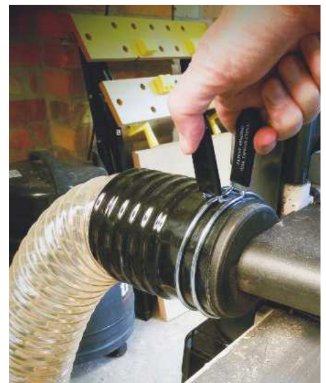
3 Axminster's quick-release hose clips make moving the extractor around simple
