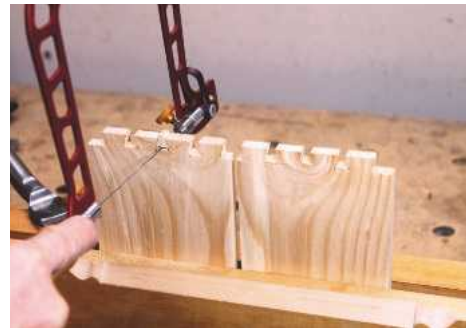
8 Saw at a steady, unhurried pace, taking care not to overshoot and mar any edge
