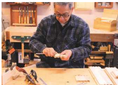
12 Scribe the grooves with a marking gauge, which would give cleaner edges whether you chisel or plough
