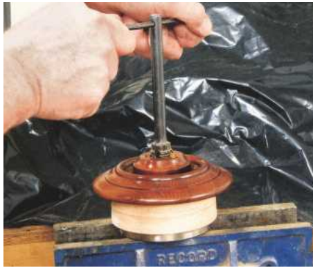
12 Hold the base in a vice while you tap the thread
