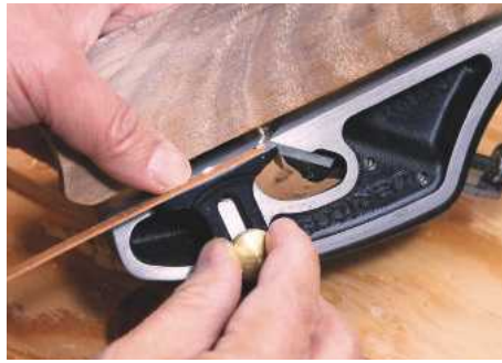
4 The inlay itself can be used to set the rebate plane's depth of cut – no measurements needed
