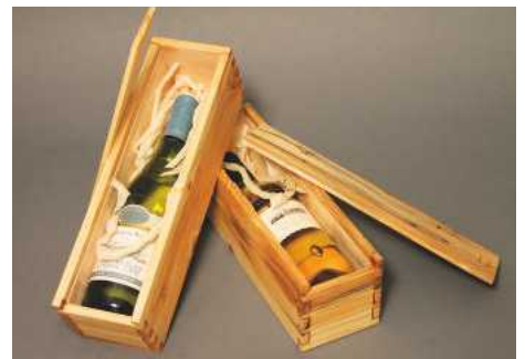
24 The completed inlaid dovetailed wine bottle box
