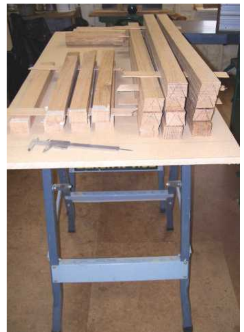
7 Laminates cut and stacked in their sets, ready for gluing up
