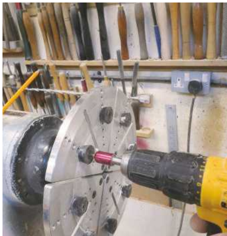
23 These type of jaws are available for most makes of chuck and are certainly an asset in the workshop when it comes to working on the bottoms of bowls. The drill makes moving the buttons from one position to another very easy
