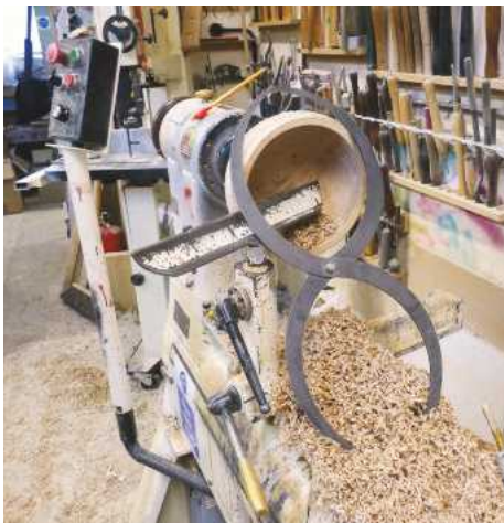
19 I see a lot of ruined bowls online, which could be avoided by some simple measuring using the figure-of-eight callipers. The large size of these custom-made ones allow me to get right into the base of the bowl
