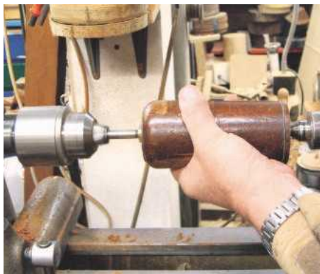
15 Put the lathe on a low speed and drill the holes both ends
