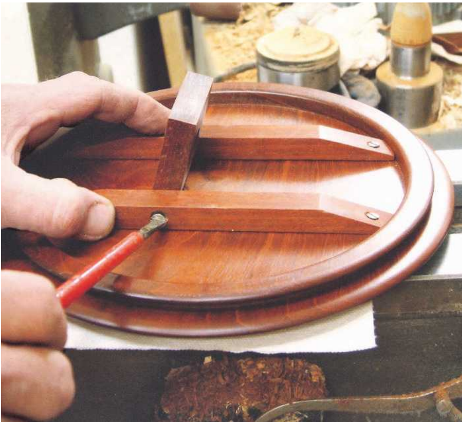
8 Pre-drill all the holes before you screw it all together
