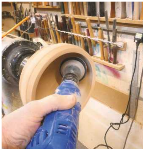
20 Power sanding, in my opinion, is the most effective way of preparing the inside of the bowl for finishing, and the 75mm Hope Woodturning sanding pad is perfect for this when coupled with a power drill. I use the drill in the 3 o'clock position on the inside of the bowl
