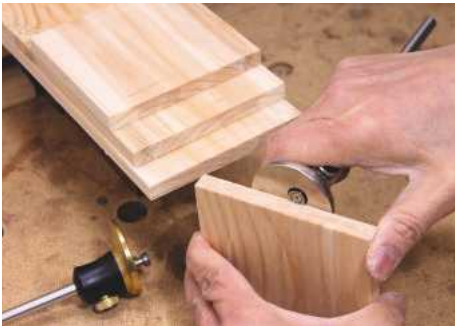
3 To use a shoulder plane to rebate, scribe out the rebate, and clamp a batten to guide the plane
