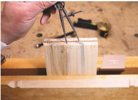
6 Mark out the top and bottom grooves on the end-grain so you can position the half pins in alignment with the grooves
