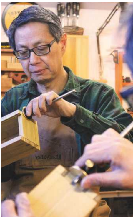
22 To highlight the hand-made character, make the faint layout lines visible
