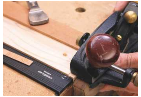
5 The scribed line on the face can be used to set the rebate plane's fence
