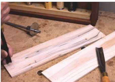
21 A hand-carved finger hold adds a bespoke element to the work
