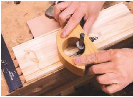
15 For better control of the router plane, use a sharp cutter and set it for light cuts
