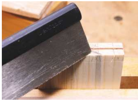
7 Check that the guide kerf is square across on the end-grain before sawing to the slope
