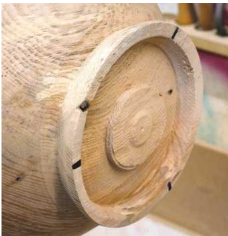
25 Just before I started cutting away the unwanted wood, I realised that one of the feet would be weak due to the grain direction, so I remarked their position. As I've lost some of the spigot, I may not be able to achieve the curve I first envisaged
