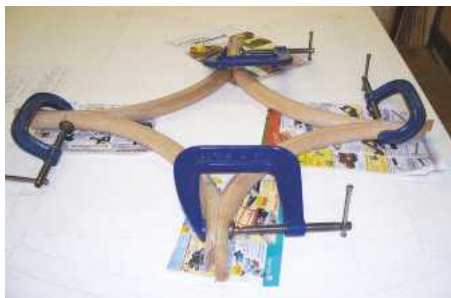
10 Bottom rails being checked against the rod, then glued together
