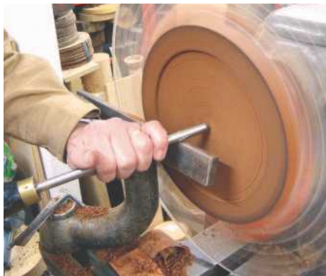
1 Turn the underneath of the top with a 9mm gouge, keeping it as even as possible
