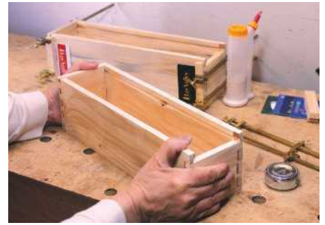
16 Before clamping, press on the opposite corners until the two measured diagonals become equal
