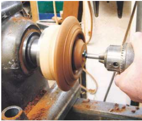
11 Slowly drill a hole in the base for the thread; make sure the lathe is on a low speed
