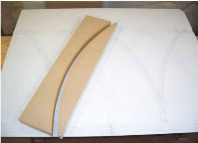
4 Leg laminating mould being checked against the rod
