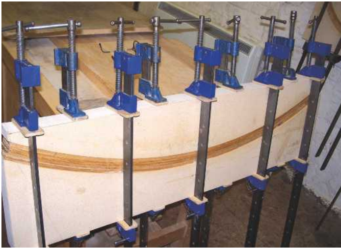
8 Laminated leg glued up in mould
