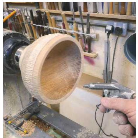
21 Ash is one of the timbers that tends to be fairly easy to sand, but its open-grain means that any abrasive which comes off the cloth will be trapped. This can lead to scratches, so a blow out with compressed air between grits is advantageous in terms of avoiding this
