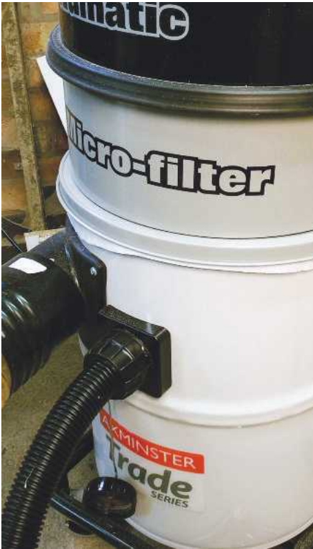
4 Swapping to the smaller hose means I can connect the same extractor to my router table
