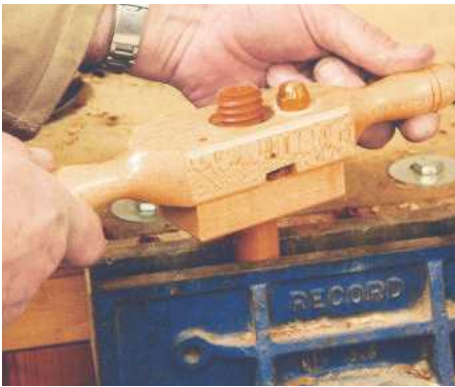
19 Hold the dowel in a vice while you cut the thread
