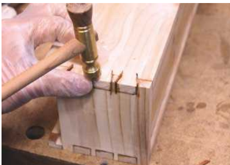
20 Press the inlay against the kerf as you hammer the strip home
