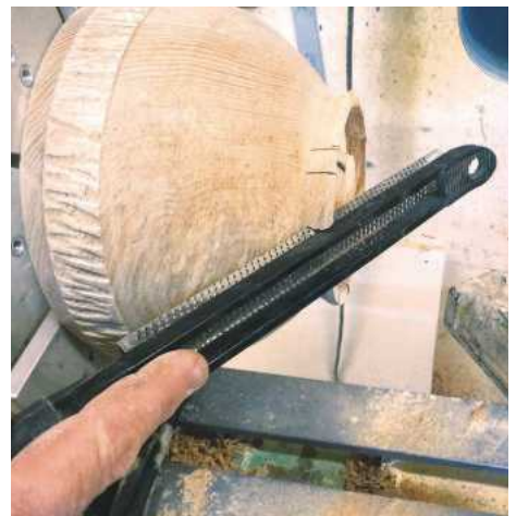
27 These Microplanes are so sharp that they remove the timber really easily. Ensure to not put too much pressure on them as being this sharp means they therefore aren't as robust
