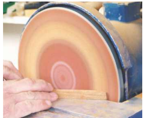
7 I used a disc sander to shape up the ends of the cross-members
