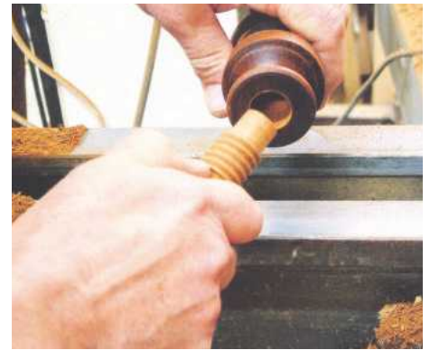
21 Apply a little PVA and glue it into place
