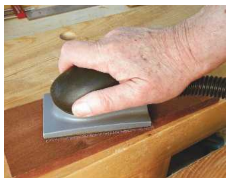
17 For dust-free hand-sanding, I like Mirka's Abranet abrasives and extracted sanding block
