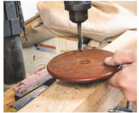
13 Mark out three equal spaces and drill the holes for the feet
