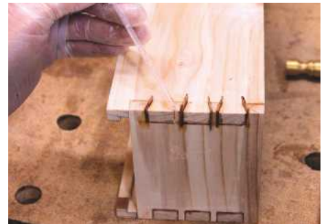
19 To keep the inlay strips from swelling, CA adhesive is dispensed into the kerfs, not onto the strips
