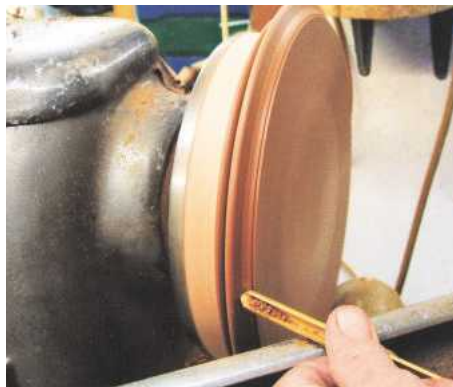
6 Use a 6mm gouge to slowly form the profile on the outer edge
