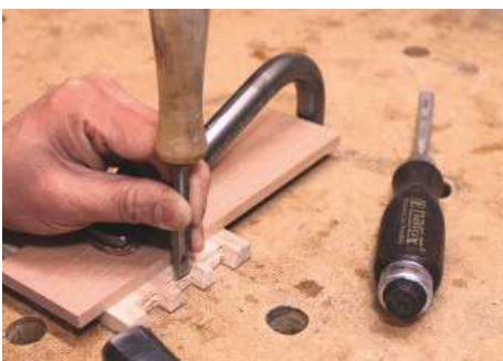
11 When chopping to the shoulder line, angle the chisel very slightly to undercut the tail socket
