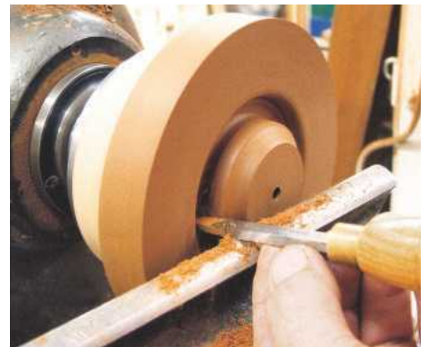
9 A 6mm scraper is ideal for turning the concave in the base
