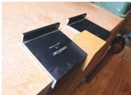
The simple dovetail marker offers a full 20mm square line, meaning that both rake and square line can be marked without moving the marker for stock up to this thickness. Much less fiddly than this Veritas equivalent, which must be used with a square
