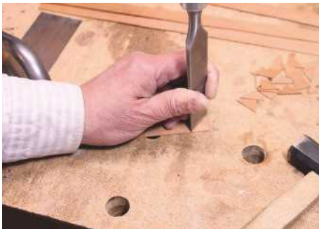
17 Cut a few narrow inlay strips, and chop out the inlay triangles
