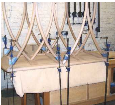
12 Gluing the legs to the table top
