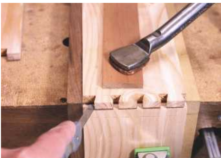
9 British woodworker David Barron's style of dovetail alignment board is used to mark the pin boards
