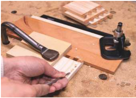
14 Drill a blind hole on either end of the groove to act as a stop to guide the chiselling work
