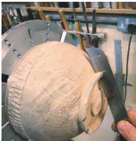
26 The feet have been marked out and the fine-tooth saw is used to cut down the side of the feet being careful not to mark the curve of the bowl. Lock the spindle of the lathe to stop the bowl revolving
