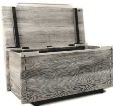
A functional blanket chest in Douglas fir by Alan Peters with distinctive protruding tenons that allow for timber movement
