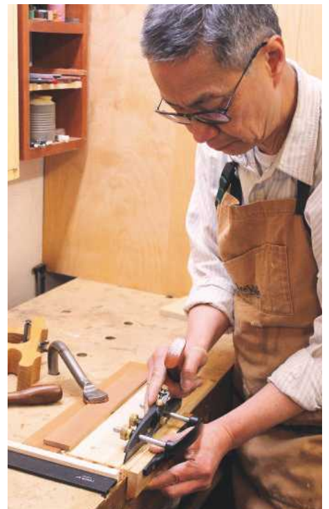
13 In ploughing, start from the front end, gradually taking longer and eventually full-length strokes
