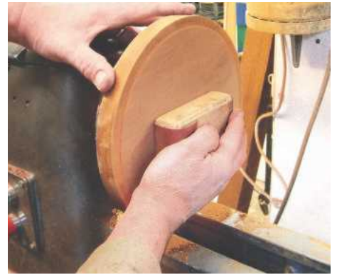
5 Sand the top by wrapping abrasive around a cork block, sanding with the grain
