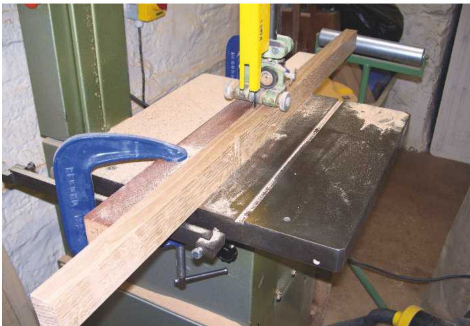
6 Cutting laminates on the bandsaw
