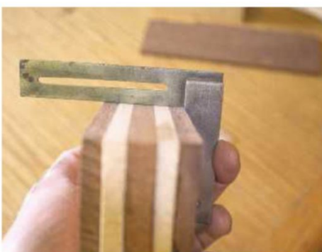
13 ... and then cleaned up and checked for square
