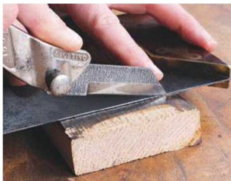
24 Marking with the slitting blade mounted at 30°
