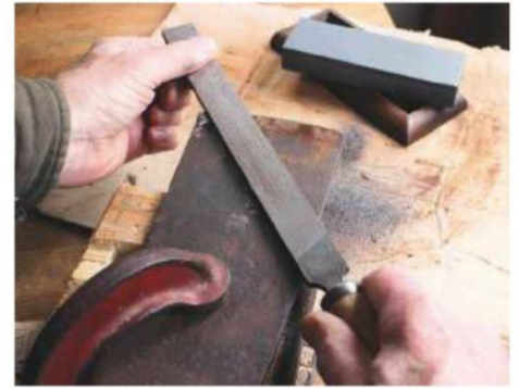
17 Filing the corroded back of the slice
