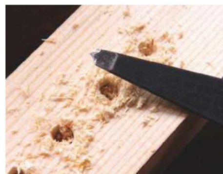
31 Centre-point bradawl shaped from a screwdriver blade
