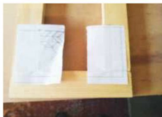
10 If you place the graph paper carefully, it will stop the glue oozing onto your bench
