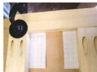
8 ... then screw it with a low torque setting so you don't force the joint
