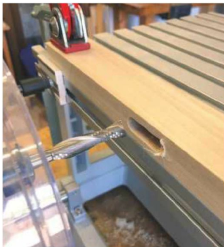
The completed mortise
