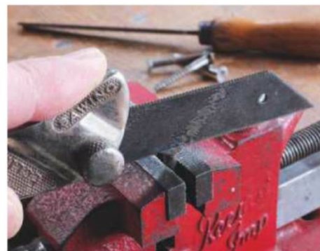
26 Renovating screws with a chisel-toothed slotting blade
