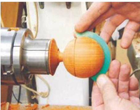
16 ... for checking that the lid and body are close to being as spherical as possible
