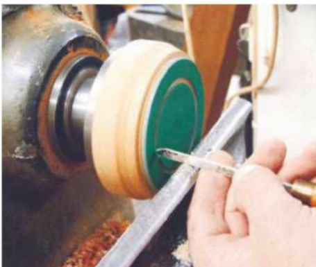
10 Before turning the body, make yourself a template from scrap plastic, then...
