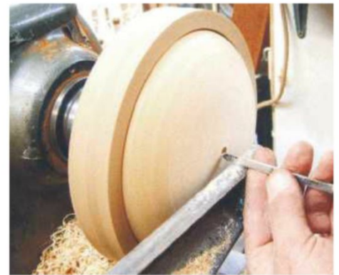
8 You can use a small parting tool to turn the hole for the spigot
