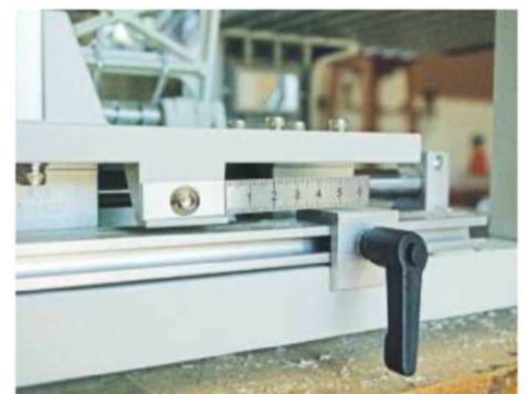
The depth stop is very simple to adjust and lock
