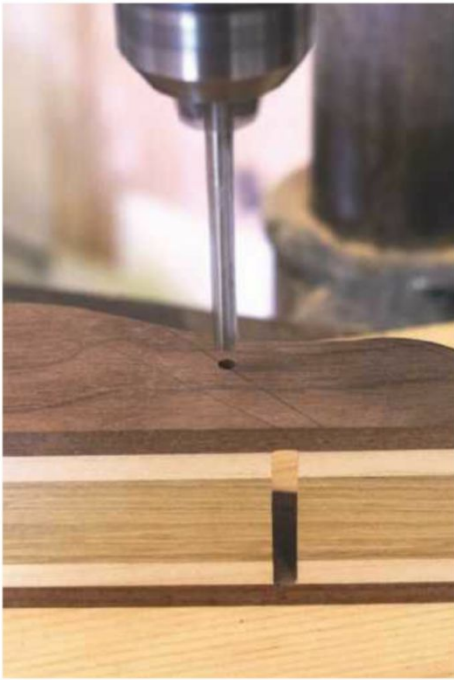
24 The body must be square to the drill for accuracy through both sides
