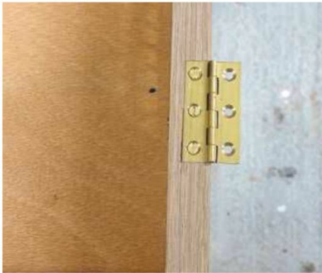
9 50mm brass hinges let in by hand
