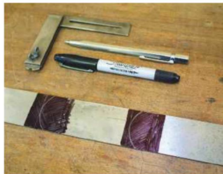
2 Tool steel marked for cutting
