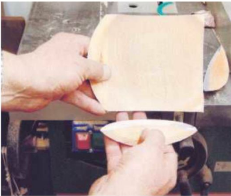
9 The scrap wood will break away easily; you can sand the edges by hand
