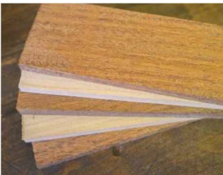
10 Prepared strips of wood, ready to be laminated
