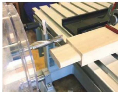
The completed tenon
