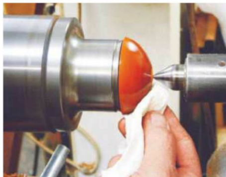
17 Reverse the lid and fix it into the combination chuck, or a jam chuck, to finish it
