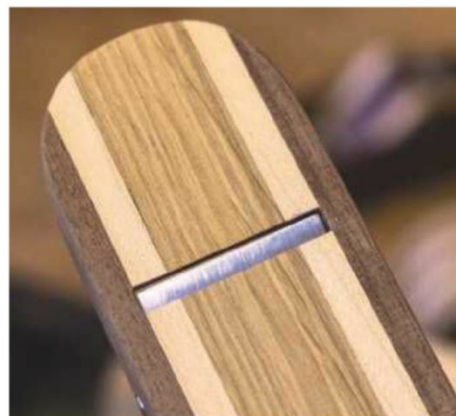
33 The finished plane should have an even opening in front of the blade...
