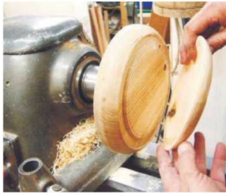
6 Reverse the base into a homemade jam chuck, making sure it's a tight fit
