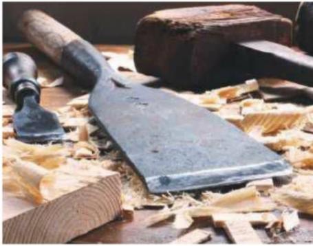
15 The shipwright's slice dwarfs a 35mm butt chisel
