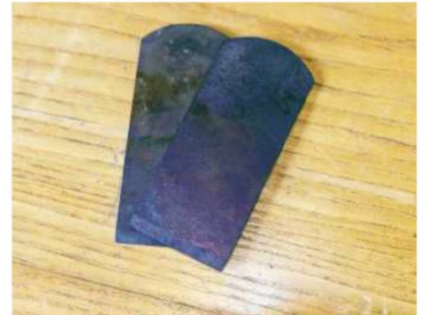
9 Tempering changes the colour of the metal
