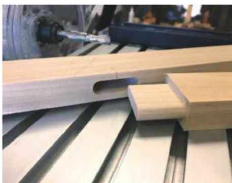
The result is a nice crisp mortise & tenon joint
