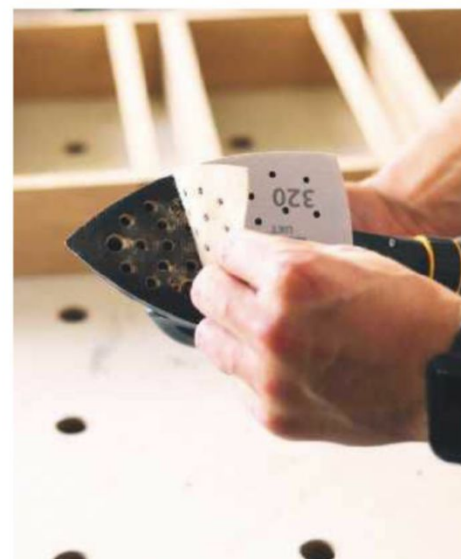
Changing of sanding sheets while using a base saver pad with plenty of extraction holes
