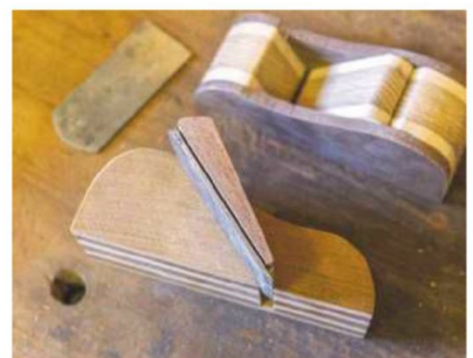
23 Laying the blade and wedge out allows accurate positioning of the bar
