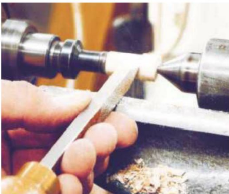
19 Turn the spigot that connects the box to the base between centres with a parting tool
