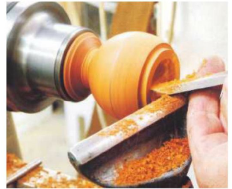
14 Use a 12mm scraper to turn the inside – the sharper the tool the better!
