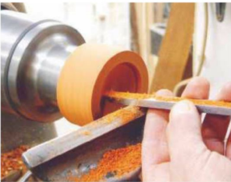
15 Next, mount the lid into the combination chuck. Again, use a scraper to turn the inside. This is where your template comes into its own...
