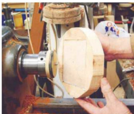
3 Drill a pilot hole and mount the blank onto a screw chuck
