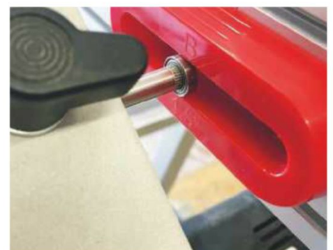
To cut a mortise, the bearing-guided follower is positioned in the centre of the template
