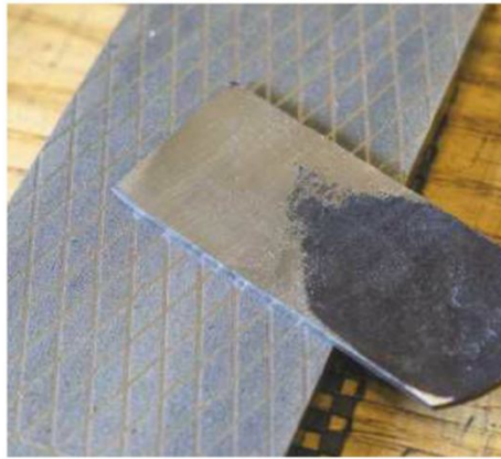
25 The back of the blade is flattened...
