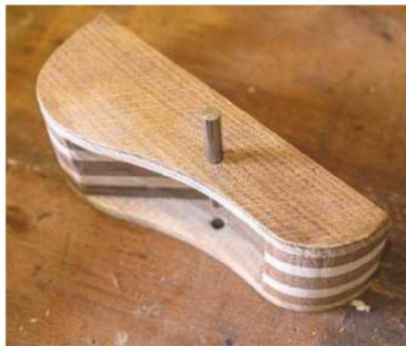
28 1/8" steel bar is a nice tight fit in a 6mm hole
