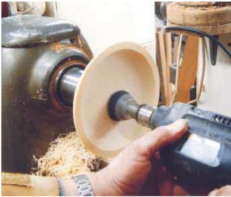
5 I used a power sander to achieve a good finish on this fairly large, flat area
