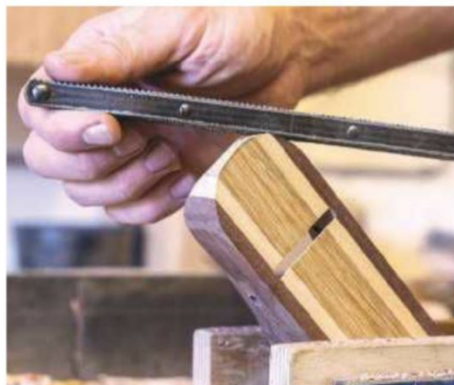
30 Final shaping is carried out using a saw rasp
