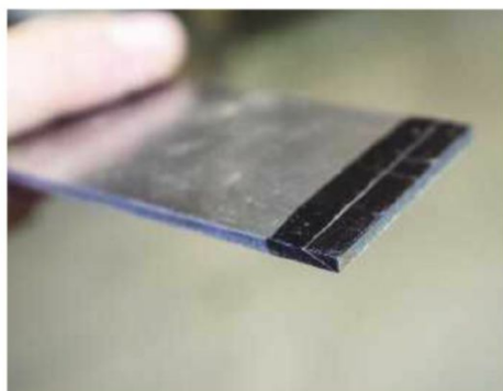
4 The bevel angle is marked on the blade blank...
