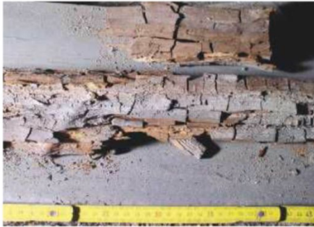
Wood decay caused by the brown rot fungus Serpula lacrymans (true dry rot)
