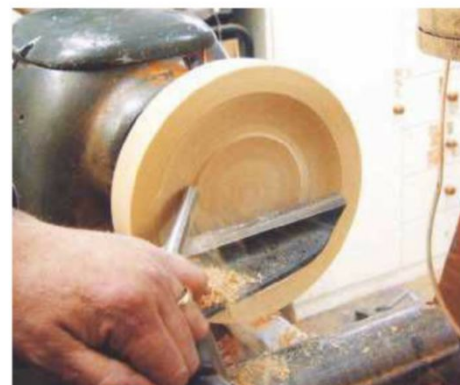
4 Use a 9mm gouge to turn the underside of the base
