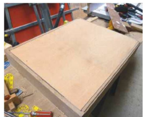
5 Plywood back fitted into the carcass
