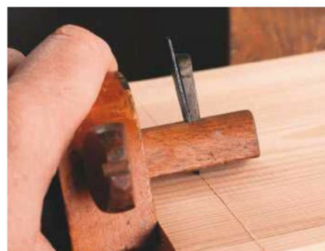
5 Cutting a shoulder line before rabbeting across the grain
