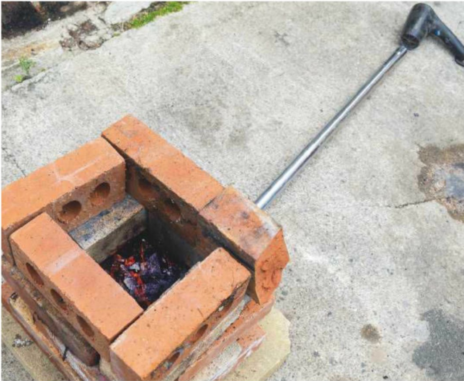
7 A homebrew charcoal-fired forge is enough to get steel red hot
