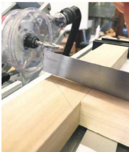
A little fine-tuning of the table would be required to cure the slight misalignment of the joint
