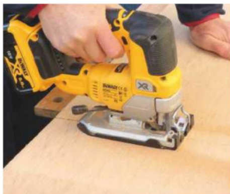
23 Cut the MDF with a jigsaw fitted with a suitable blade. If provided, fit a plastic shoe over the baseplate when sawing veneer
