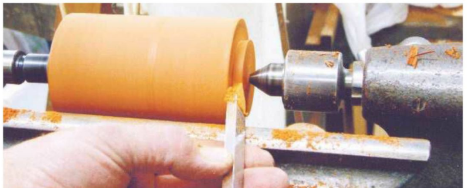
11 ... mount the padauk blank between centres and turn dovetails to fit a combination chuck
