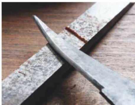
27 The curved two-edged scraper removing rust
