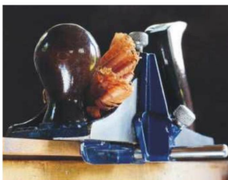
4 The rabbeting gauge clamps to the side of the plane
