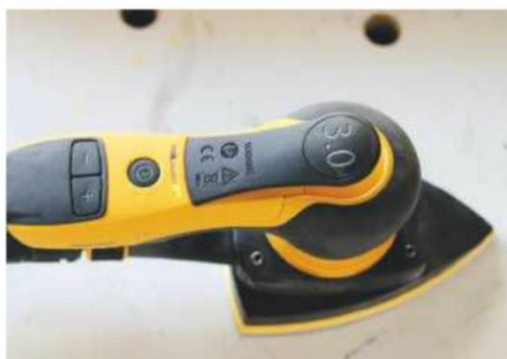
The plus and minus buttons allow you to set a maximum power level
