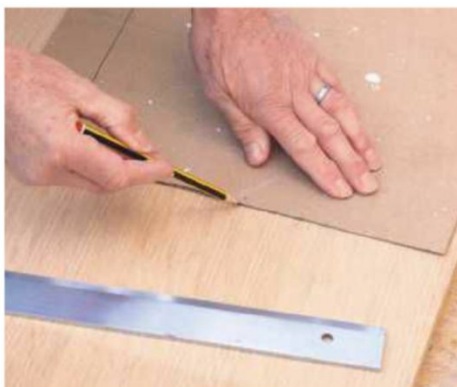
22 Trim the template for a snug fit, then position it on the MDF. Draw around the ends, keeping it away from the rear edge of the board
