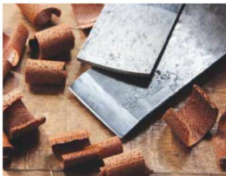
28 A flat scraper was ground to make a 19mm chisel
