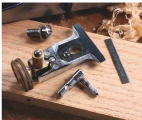
3 Blade clamp with thrust block and spindle-cam exposed
