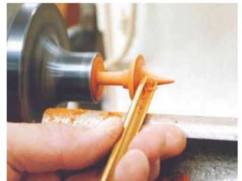
18 Take your time when turning the finial, so as to keep it crisp and sharp
