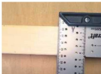
1 Marking the cut
