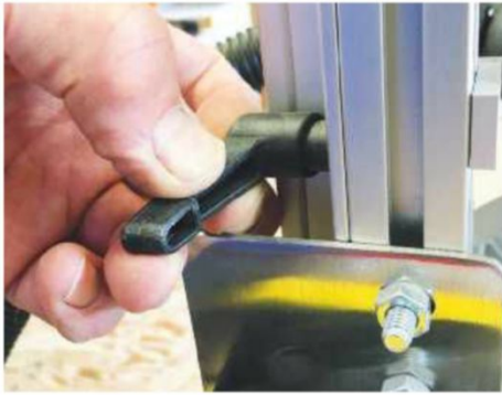
Annoyingly, some of the Bristol lever adjusters clash with other components
