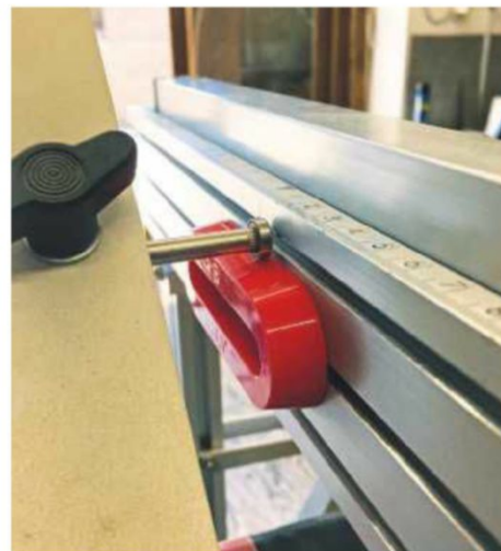
To cut the tenon the bearing follower is repositioned on the outside face of the template – note the clever tapered edge for fine adjustment
