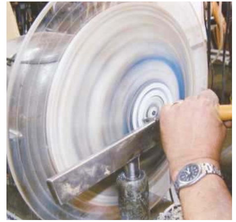
10 Reverse the bowl into the jaws and turn the spigot into a foot
