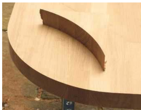
With a couple of curved units in my new kitchen, the jig's 250mm radius was a pretty close match
