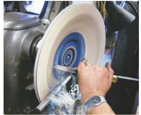
6 Use a 12mm gouge to turn the inside and watch the pattern of the JAZ's layers reveal itself
