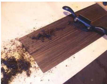
7 A scraper plane can be used to thin the ribs
