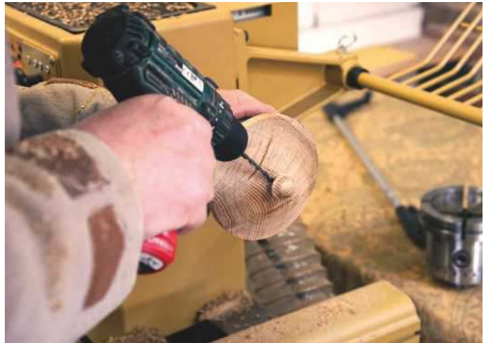
17 Using a 10mm spindle gouge, I turned a bead and knob for the top; this would allow the bird box to be drilled to accommodate garden wire for hanging in a tree
