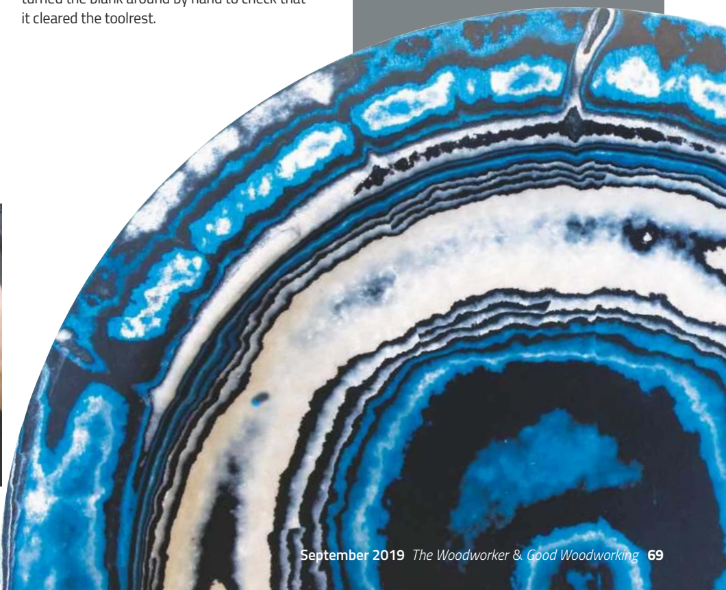
7 In the event of delamination, cut off the loose part and re-turn the surface to remove the flaw
