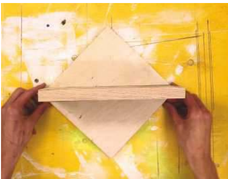
10 Mounting the horizontal piece onto the back mounting piece
