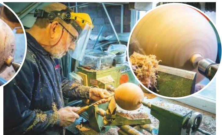
John turns away the high spots, the tool guided by the ghosts created along the horizon of the rotating wood by irregularities on its surface
