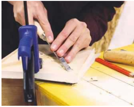
15 Embedding two keyhole hangers into the back piece to ensure it lays flush against the wall
