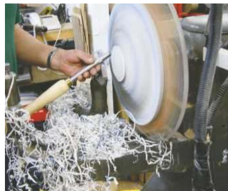
3 Turn the spigot with a parting tool and shape the rest of the bowl's underside with a gouge
