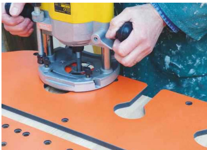
You don't actually need a jig for installing connector bolts, though this does speed up the process
