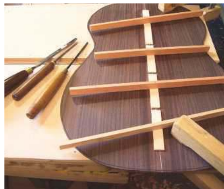
26 Housing slots are cut in the centre strip for the back braces
