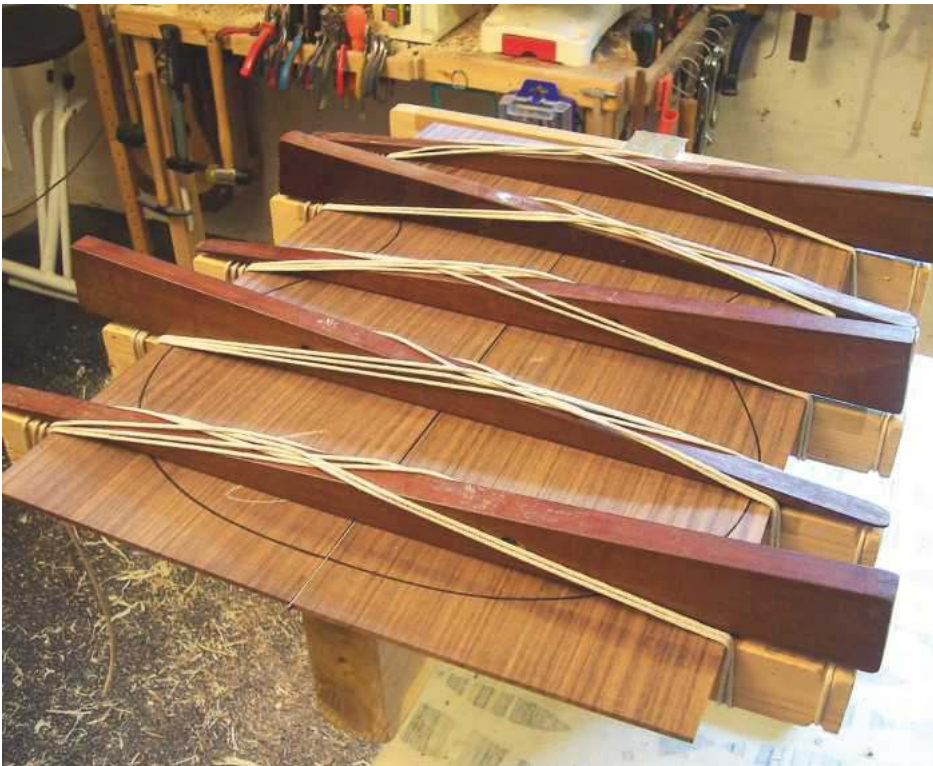
20 The back in the wedge and lace jig with centre inlay
