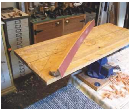
25 The curved sanding stick, which creates a 3mm 'lift'
