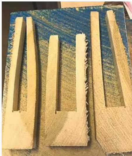
These test pieces show varying degrees of case hardening
