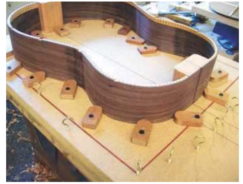
12 The heel and tail blocks dry fitted
