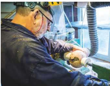
... the fixed centres making way for cups that allow the sphere to be freely repositioned
