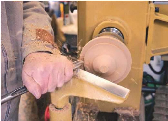
16 Using a bowl gouge, I turned the top to a pleasing shape that would easily throw the water off – in this case, I chose to mimic a pagoda
