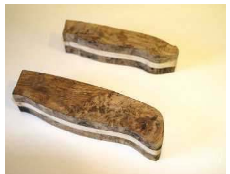
10 Once cured, the edges can be trued up
