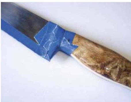
19 Once assembled, the tape is wiped and removed
