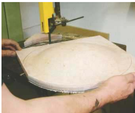
1 Mark out a circle on the blank and cut it out on the bandsaw. The easiest way to turn the bottom...
