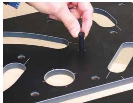
You push a pair of pins through the appropriate holes for your selected slot (external radii only)
