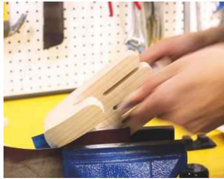
8 Abrasive wrapped around a thin piece of wood ensures the spaces between the fingers are uniform
