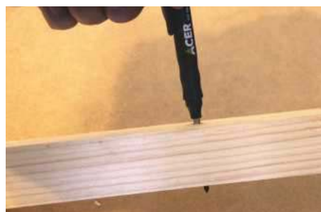
The long pen nib is ideal for marking through deep holes in timber
