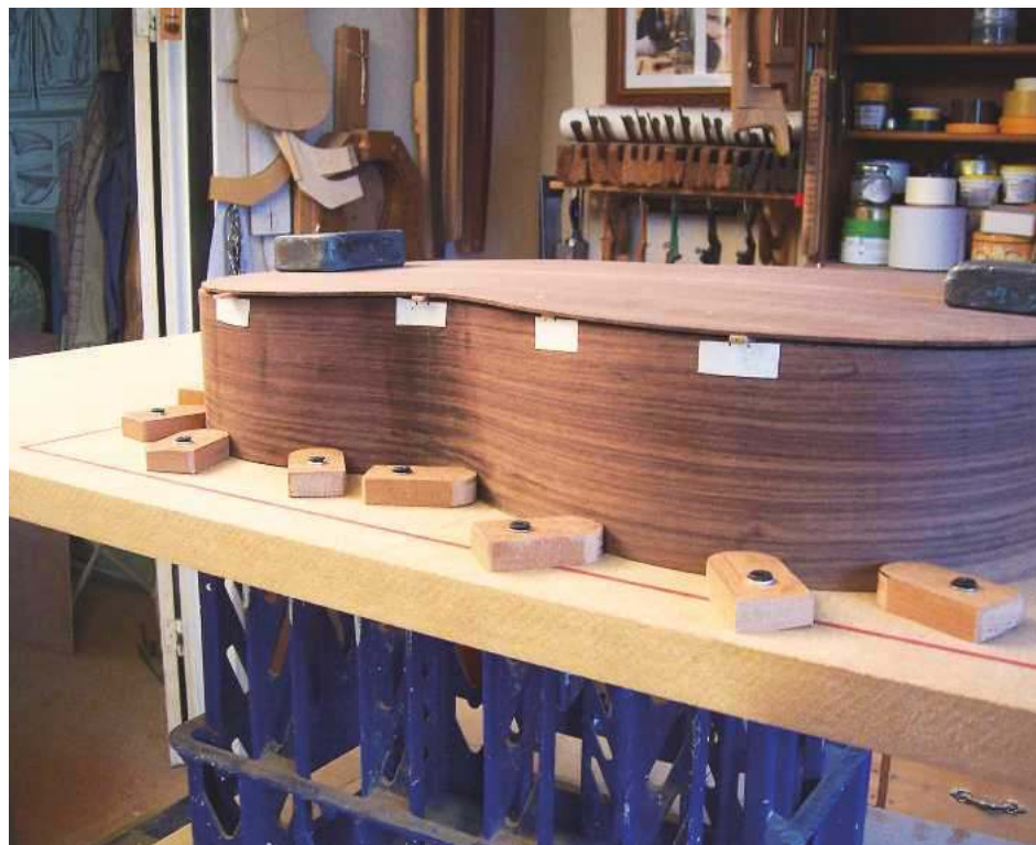
30 Small housings are cut into the ribs for the back braces
