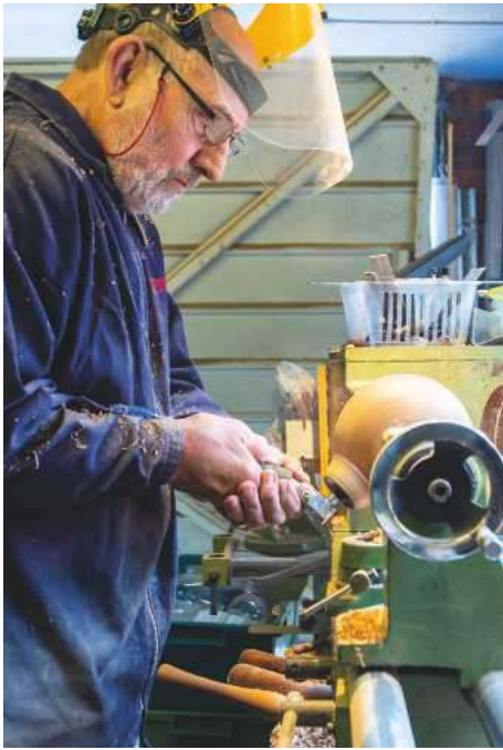
A quick sand with Abranet, and the bosses are cut away...
