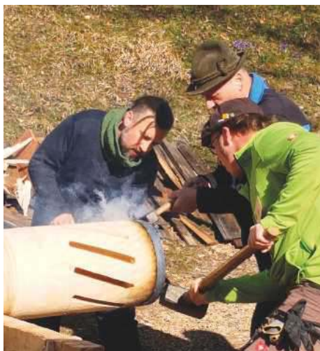
Fixing the heated metal straps
