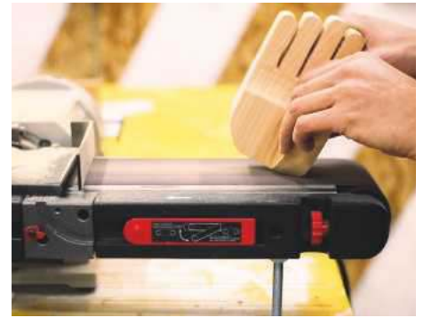
9 Using a belt sander to further shape the hand
