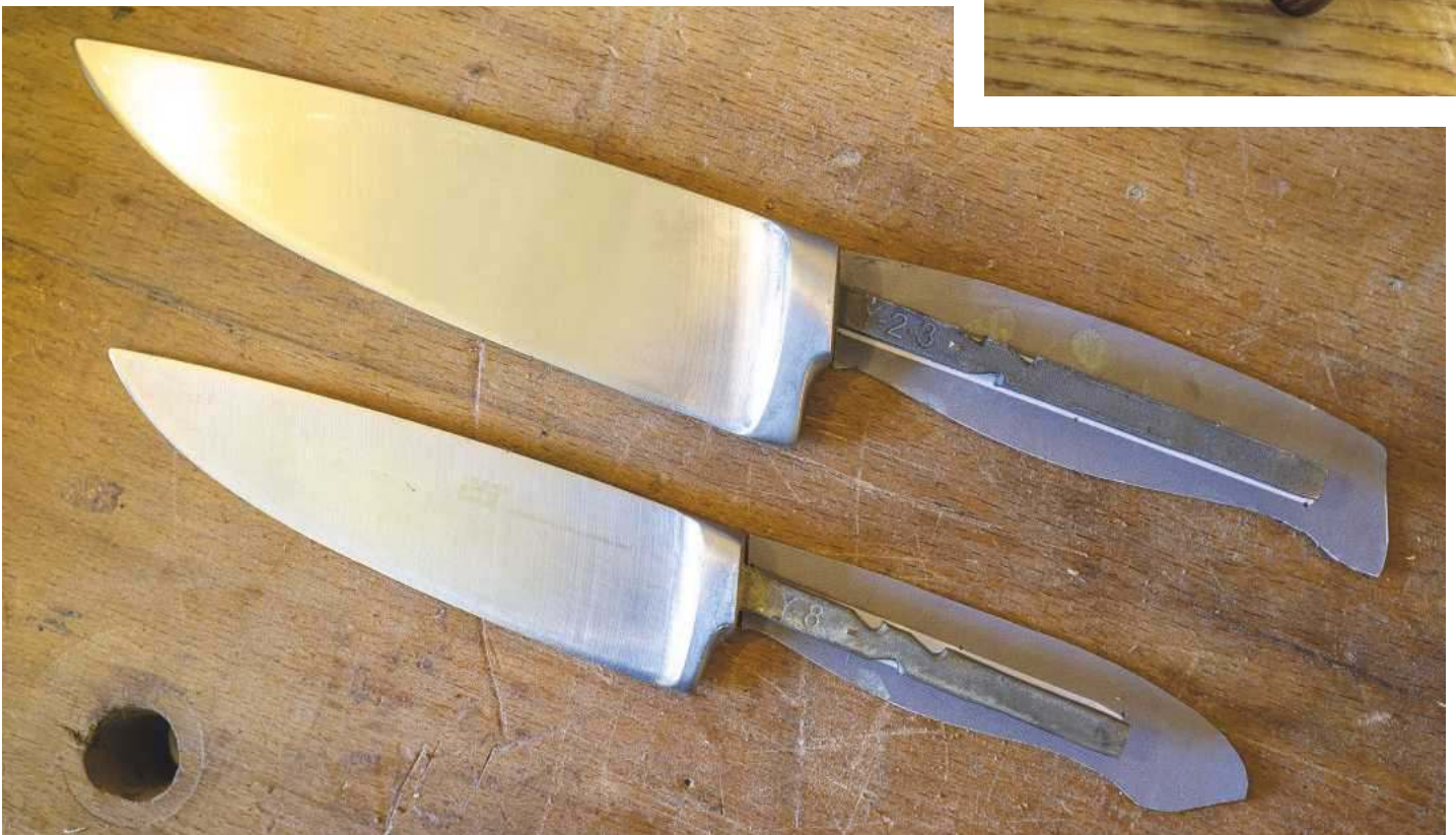
1 The knife blades have simple square tangs
