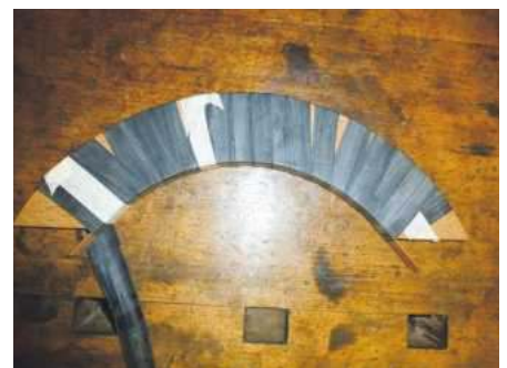
3 Wrap inner tube tightly, clamping the veneer in place
