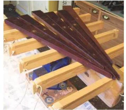
19 The wedge and lace jig for joining backs and soundboards
