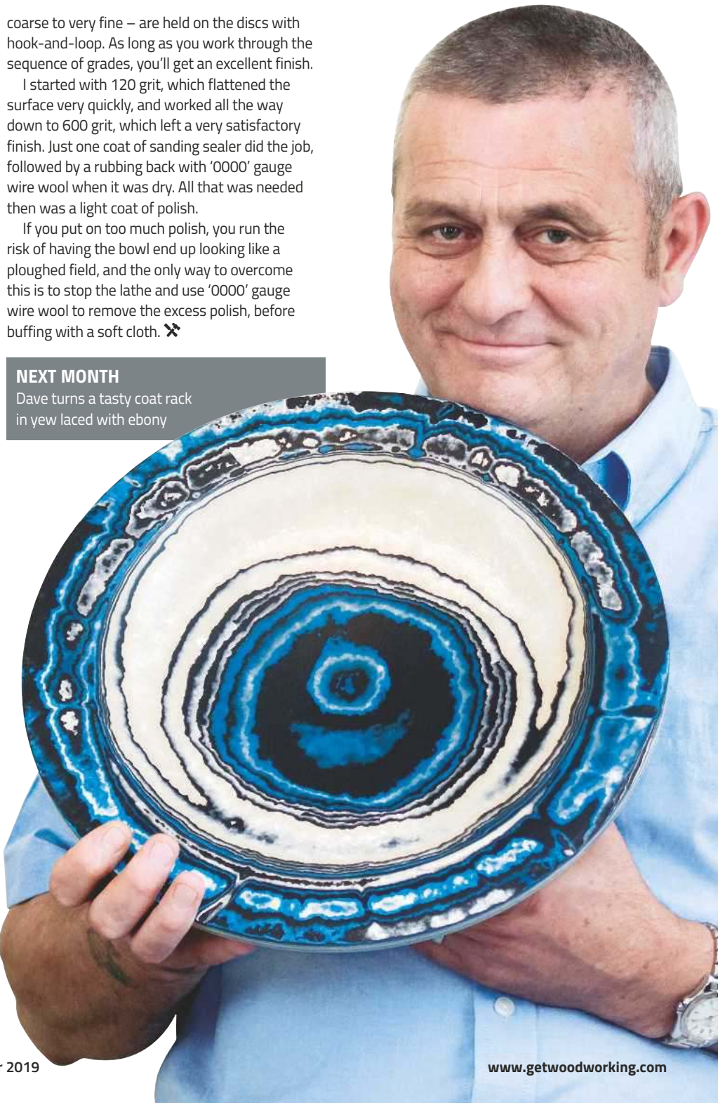
9 I found that the best and quickest way to achieve a good finish on JAZ was by power sanding
