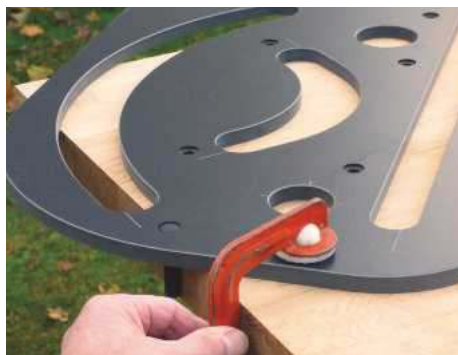
It's essential the jig is cramped securely, as a big router and guide bush could knock everything out of kilter
