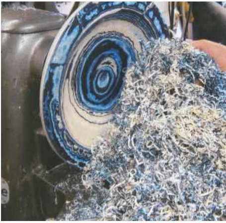
8 Correct use of the gouge will produce loads of shavings, just like a close-grained timber
