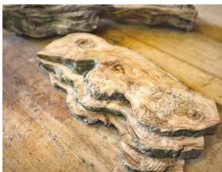
2 The oak root sliced up using a bandsaw
