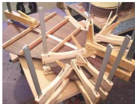
27 Clamping the back braces into place
