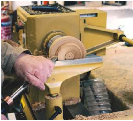
13 I cut a slight recess in the base to accommodate my large dovetail jaws; this would allow me to remove the tenon and slightly undercut the base with a 15mm swept-back bowl gouge
