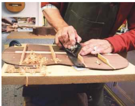
28 Gabling the back braces
