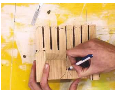
5 Marking out the rounded parts of the palm and fingers
