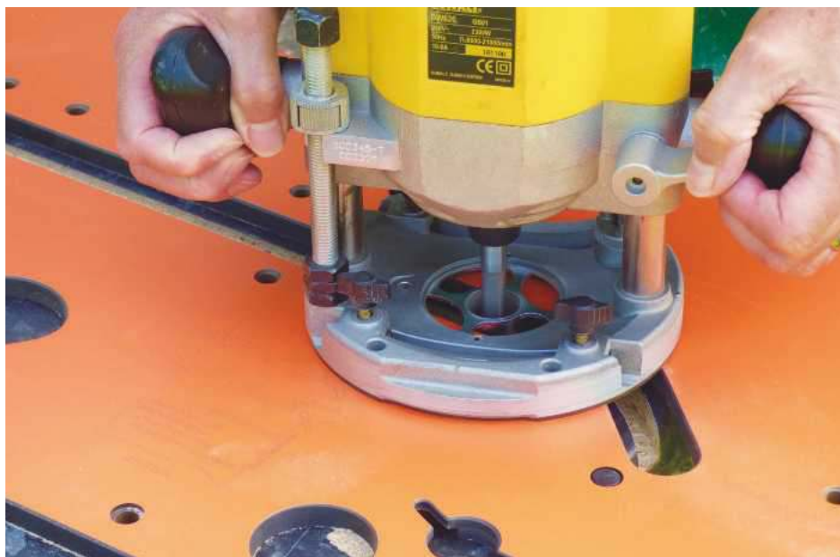
Along with a quality router bit and guide bush, you should achieve a professional finish every time
