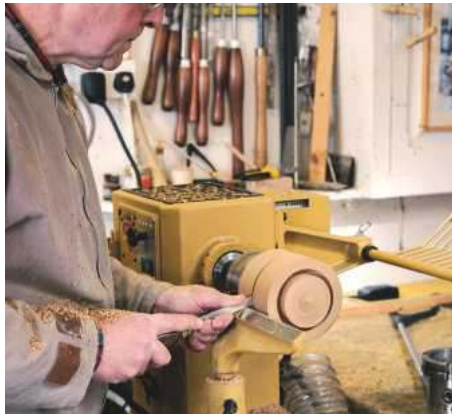
14 The offcut I had left for the top of the bird box was too large, so I parted off the material and made another base for the next box
