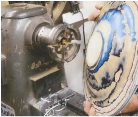
4 Reverse the bowl into the jaws on a combination chuck, and then...
