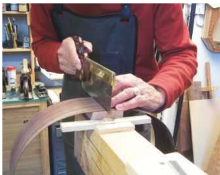
14 Sawing the tail inlay housing
