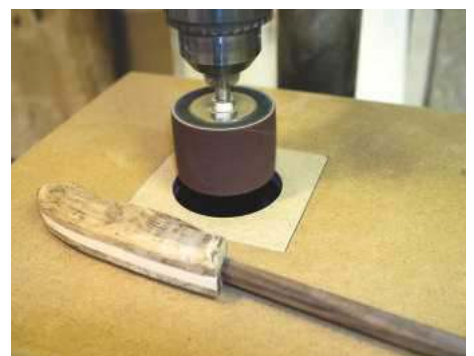
13 Final shaping is carried out using a sanding drum
