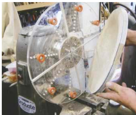
2 ... is to mount it into large jaws. I made this set myself; the hard rubber pegs hold the work firmly without damaging it
