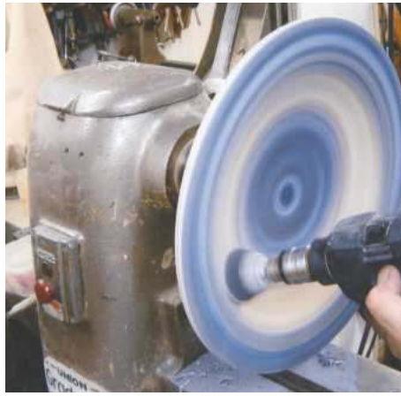
9 I found that the best and quickest way to achieve a good finish on JAZ was by power sanding
