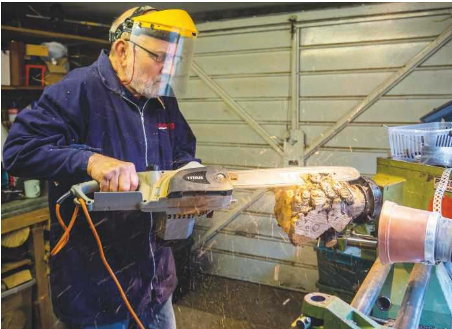
The lathe's rotating headstock allows awkward pieces to be mounted clear of the bed
