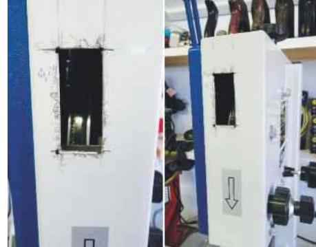
Colin's simple modification for his bandsaw – a handy observation window
