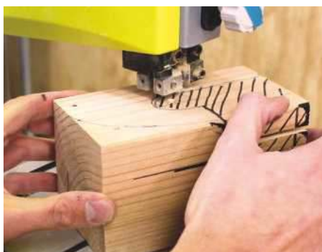
4 Cutting out the space around the thumb to reveal the palm
