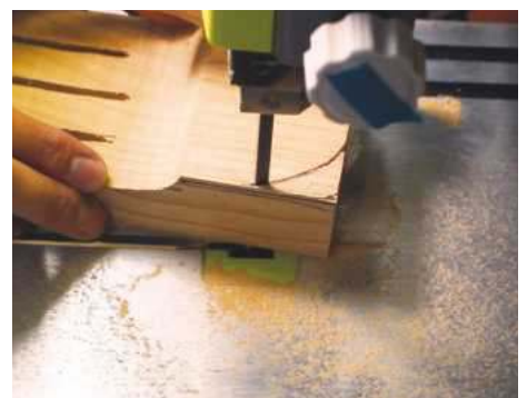
6 Rounding details using a bandsaw
