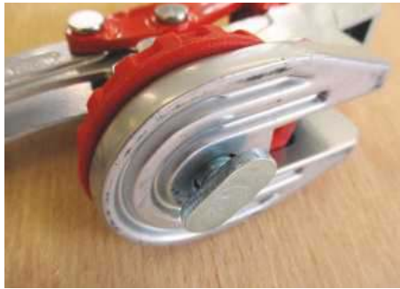
Detail of the supplied T bolt...
