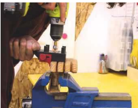
12 Drilling pocket holes in the hand...
