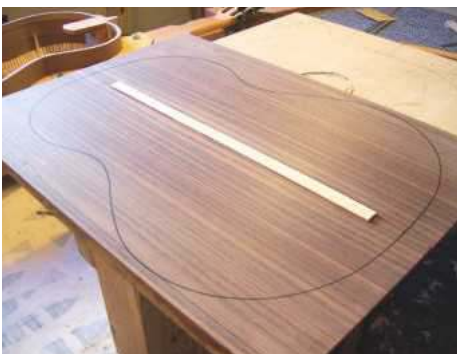
22 Back centre cross-banding strip in place
