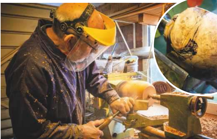
The diameter of the cylinder determines the size of the finished sphere; with a pencil-line as an equator, the ends of the blank – the northern and southern hemispheres – can be shaped to curve down to the 'poles', where John has turned a pair of bosses to mount the workpiece between centres
