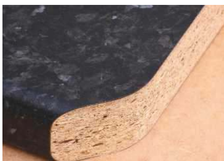
However, the problem with plastic laminate chipboard worktops is that front edges are usually rounded over, or postformed
