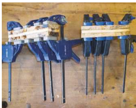
9 The layers sandwiched together and clamped
