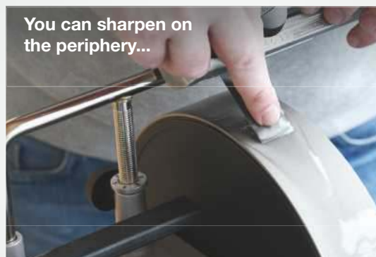
Gouge sharpening with the SVD-186 Gouge Jig.
