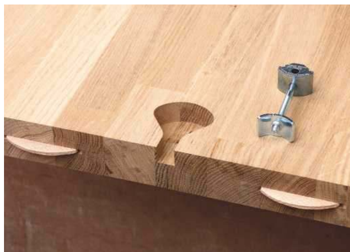
Cut slots between bolt positions and glue the biscuits first, though don't use PVA adhesive if worktops are chipboard
