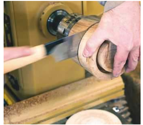
15 I always part to a dowel section of 12-15mm and then finish parting using a pull saw. I protect the teeth of the saw with a piece of material; this stops them from being broken on the lathe bed, as if the saw drops down and hits this, the teeth are very brittle and therefore likely to break
