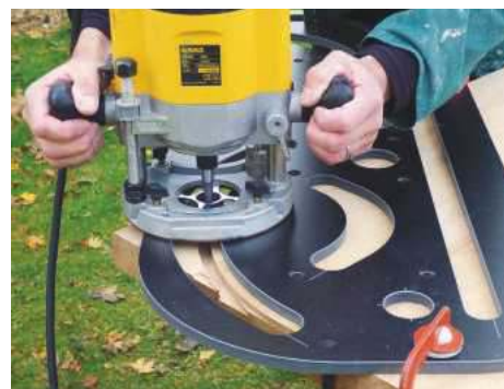
Make a series of plunge cuts down through the worktop and allow the cutter to stop before removing the router
