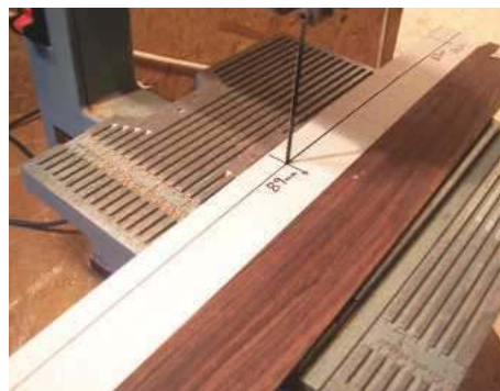
8 The correct taper is cut into ribs
