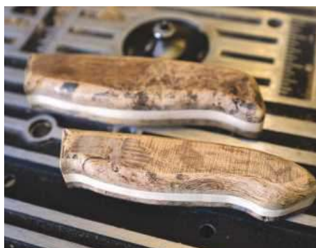
12 A router does the initial rounding
