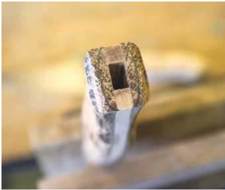
14 The handles need to match the bolster shape
