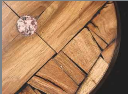
Epoxy resin can be used to combine small pieces of timber into larger boards such as the one used to make this table, which is also inset with a piece of Victory copper
