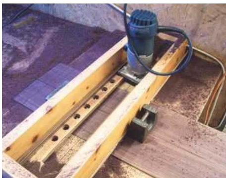
6 A homemade rib thickening jig
