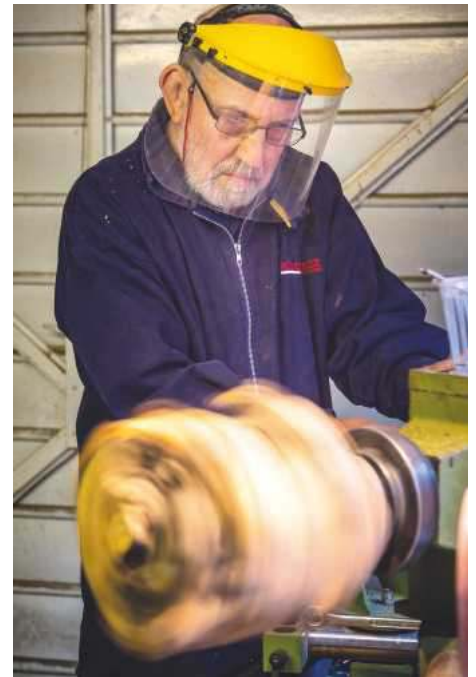
Removing the wood's most eccentric parts eventually allows the apple to be spun at a working speed
