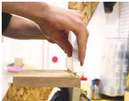
11 Once the pocket holes are drilled, place wood glue into the holes, insert the dowels and marry the two pieces up together
