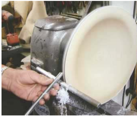
5 ... use a freshly sharpened gouge to true up the outside of the bowl
