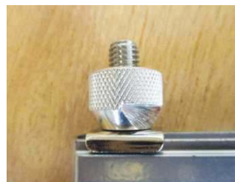
The knurled nut allows more rapid set up
