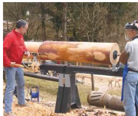
Turning a new mill shaft
