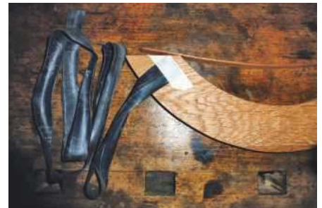
2 To start, tape one end of the inner tube to the work
