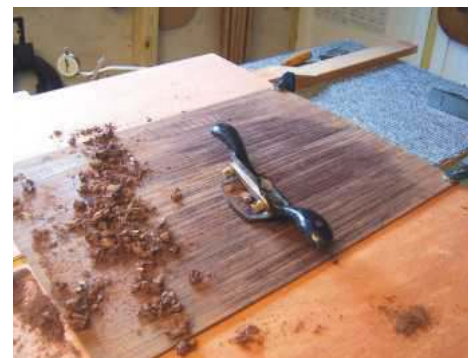
21 Thinning the back with a scraper plane
