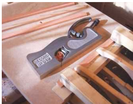
23 A shoulder plane cuts initial curve on the braces
