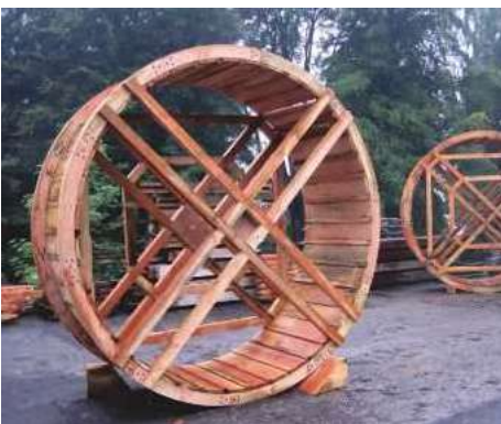
18 The treadmills have a height of 4.5m
