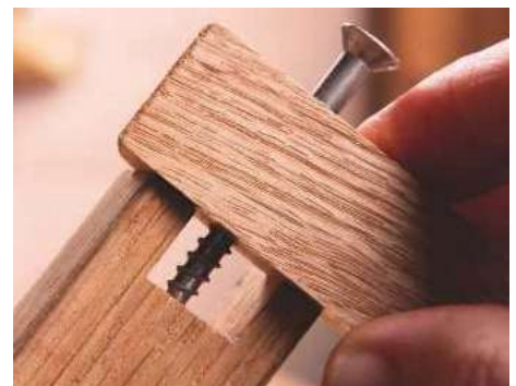
32 Testing for evenness of depth
