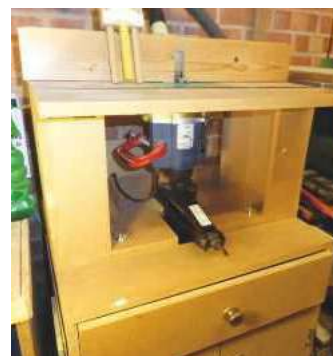
6 Router in the table with the jack in position
