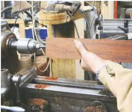
12 Drilling the column: run the lathe on a low speed and wind the tailstock in slowly
