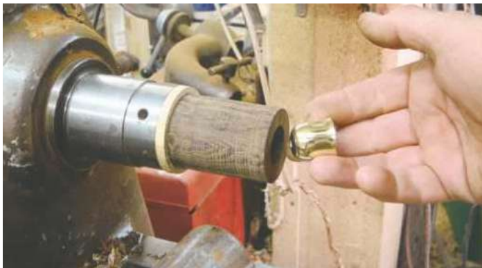
20 ... the brass insert; check the fit and don't drill deeper than necessary
