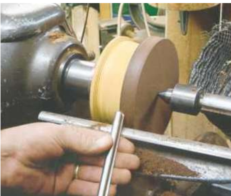
7 Hot glue the wenge disc onto a scrap piece of wood and turn the taper
