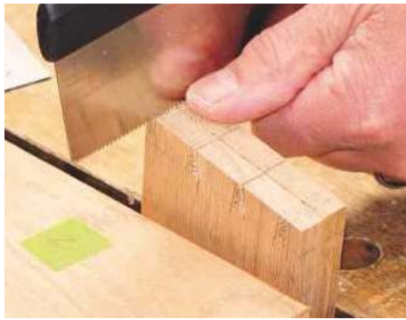
10 Secure both tail boards tightly in a vice at an angle. Cut down sides of tails with a dovetail saw
