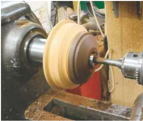
10 With the upper base ring mounted on the jam chuck, drill a 25mm hole right through
