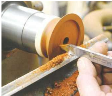
18 Turn the recess in the drip tray with a parting tool; keep it crisp and sharp
