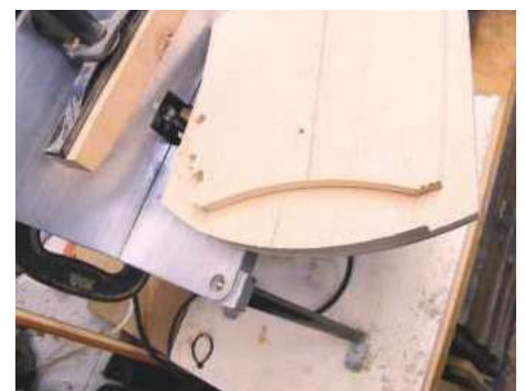
3 Use double-sided tape to secure to the template
