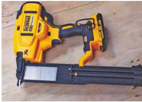
Loading the nail magazine, which takes 15-54mm 18Ga nails
