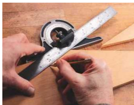
4 Using the protractor head of a combination set
