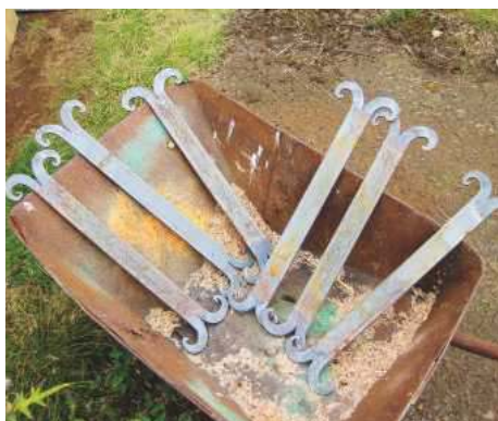
24 Hand-forged restraining straps
