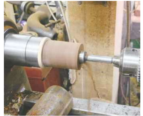
19 The scone is mounted on a screw chuck while you drill the hole for...
