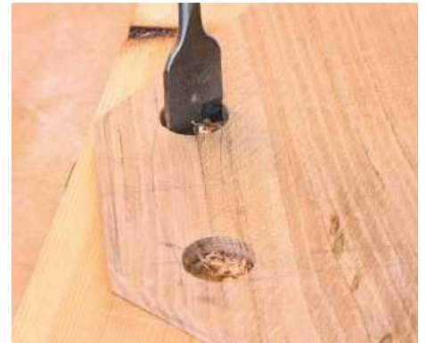
24 Mark hole centres and clamp the board to some backing material. Bore ends of the cutout with a 25mm flat bit
