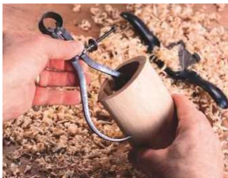
19 External callipers measuring wall thickness
