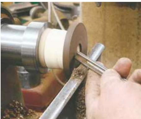
15 Jam the ring onto a jam chuck, face both sides, and then turn the taper
