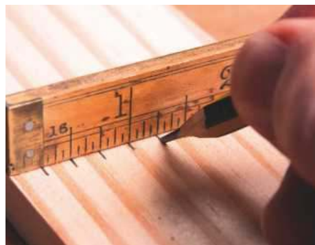
21 Marking from the edge of the rule
