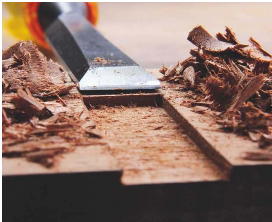
11 Dado cut to the width of the chisel
