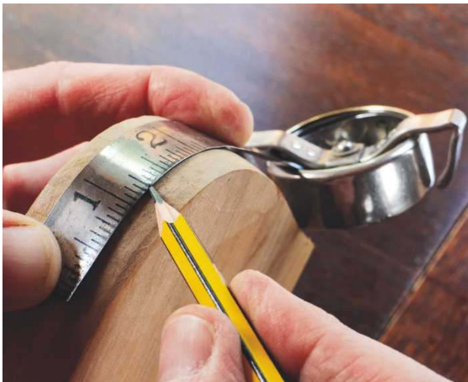
25 Working with Farrand's flexible concave-convex rule
