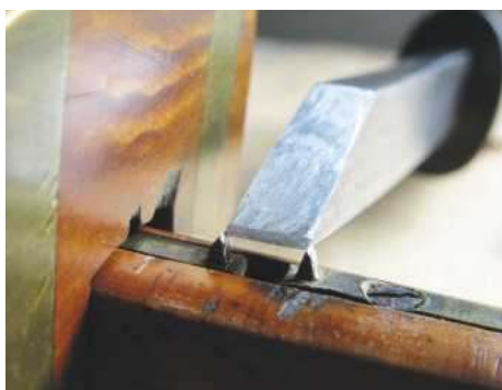
12 Setting the mortise gauge to the chisel
