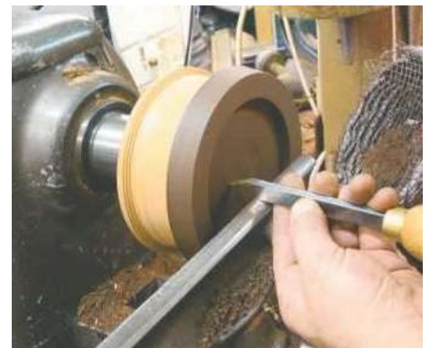
9 Use the parting tool to turn the recess, keeping a close eye on the depth
