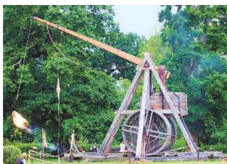
2 Warwick Castle trebuchet throwing arm, with counter weight treadmills and projectile visible
