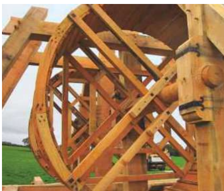
19 The treadmills rotate on axles either side of the truncated A-frames. Note the axle block
