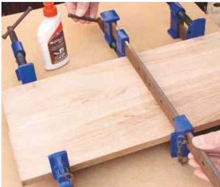
22 If required, glue boards together to achieve sufficient width for the carrying handle. Thickness when dry
