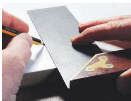
3 Testing the truth of a try square
