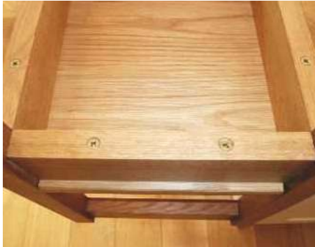
16 Attaching legs to the seat with screws
