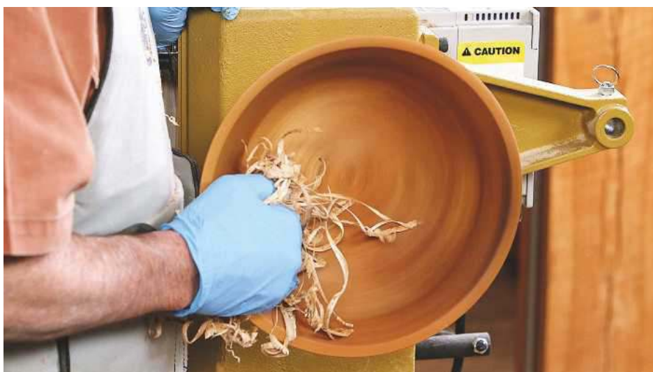
Burnishing the interior of a turned bowl using wood shavings
