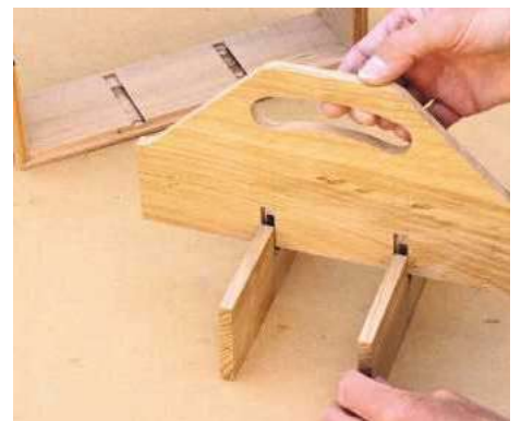
27 The handle and dividers are slotted together. Mark out halving joints and carefully cut away the waste
