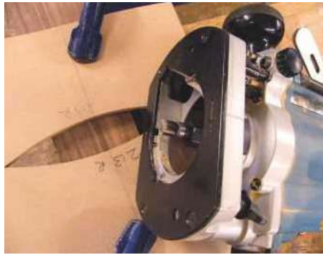
7 Secure the two templates to the walnut and cut the recess with a rebate cutter
