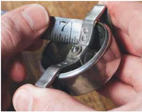
26 Safely extending the Farrand Rapid Rule
