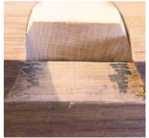
19 Pencil marks are an aid to show where the high spots are
