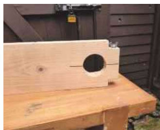
3 The jig with the appropriate size hole and restraining nut and bolt
