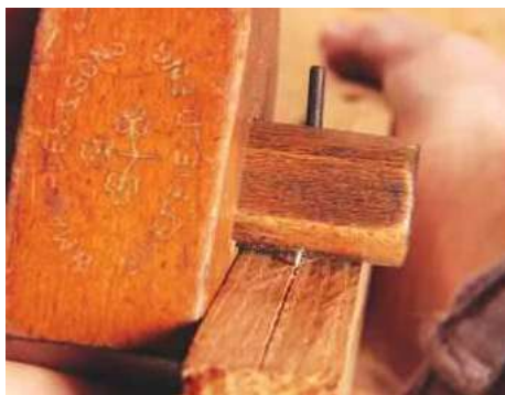
9 Scribing with the marking gauge
