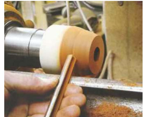
14 Hold the lower part of the column on a spigot chuck; turn the taper with a 9mm gouge
