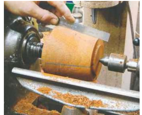
6 ... and check the taper with a steel rule
