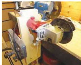
1 Angle grinder held in the jig and vice, ready for use
