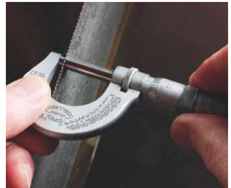
29 Measuring saw thickness with the micrometer
