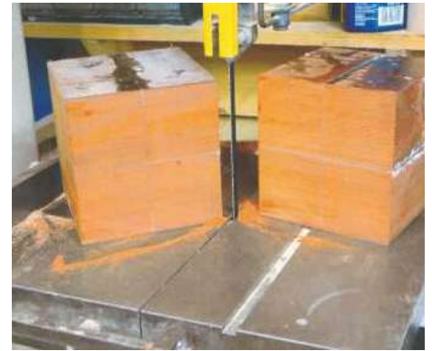
3 Saw the finished block in half and check them over to make sure the joints are tight
