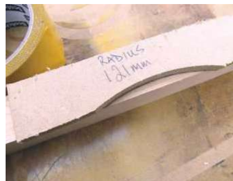
5 Secure the template to the edge of the maple
