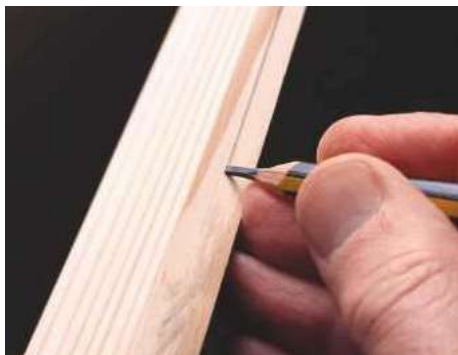
10 Marking a parallel guided by the 'fingers fence'
