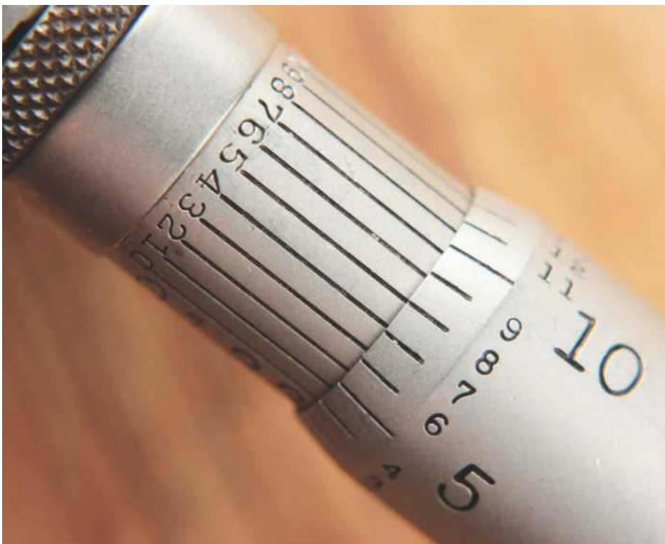
30 Vernier scale of a 'ten-thousandths' micrometer
