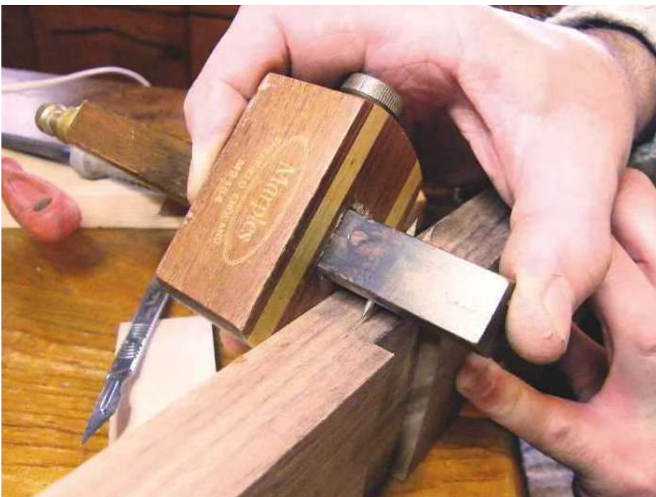
11 Use a marking gauge to set the depth of the key
