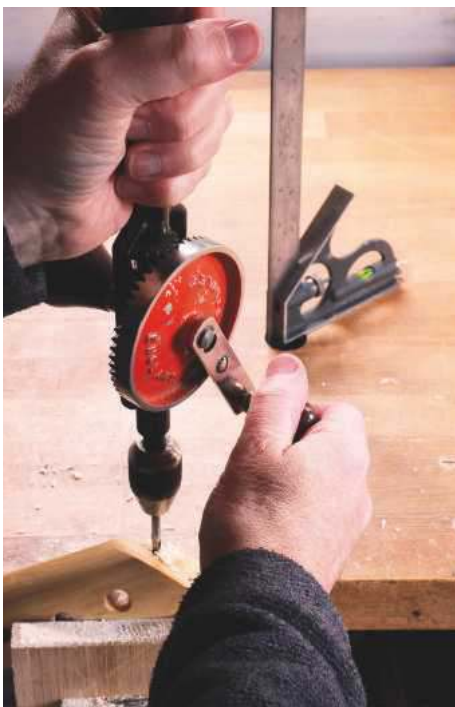
6 Vertical drilling guided by a combination square
