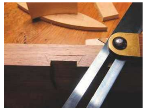
13 Use a sliding bevel to set the same angle as that at the end of the key
