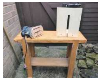
2 Circle cutting jig and guide bush guided on workbench
