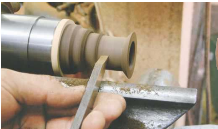
21 Use a freshly sharpened parting tool to turn the scone; turn slowly to ensure you don't tear the grain
