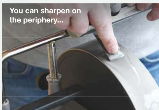
Gouge sharpening with the SVD-186 Gouge Jig.
