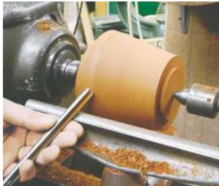
5 Turn the taper, taking light finishing cuts to achieve a good finish...
