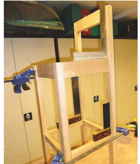
9 Checking angle alignment
