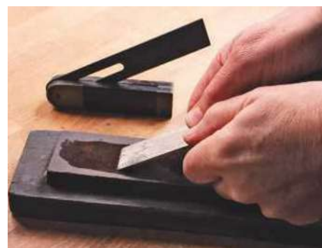
5 Sliding bevel as a visual guide to honing
