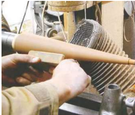
13 The quickest way to flatten the surface is with abrasive wrapped round a cork block
