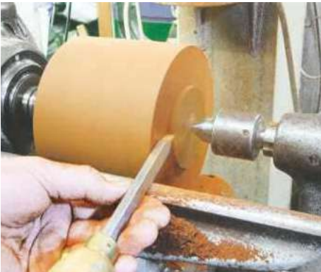
4 Mount the block between centres; true it up then turn the large spigot on both ends
