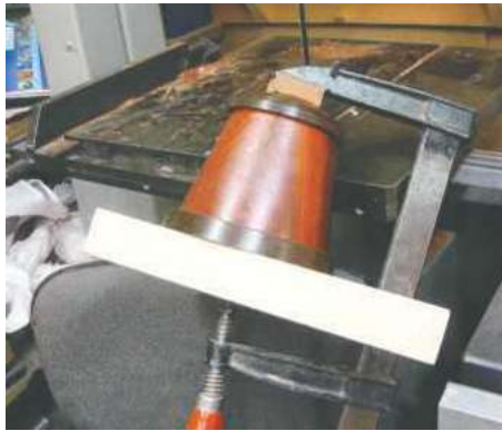
11 Glue the top and bottom rings to the base and clamp them on
