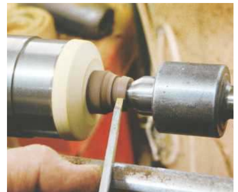
17 ... but the small ring is mounted on a jam chuck and supported with the tailstock
