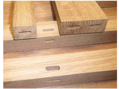
6 Mortises cut by joiner
