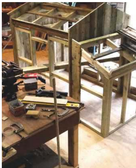
1 House under way: you need space for a thing like this. The spirit level wasn't involved: construction is by measurement. The back frame (nearest to the camera) is from lighter stock and not mortise & tenoned (overkill given its position). Instead it is half housed and screwed. I still don't like screwing into end-grain, but concede that here it makes sense. Nothing is glued
