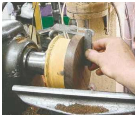
8 Check the angle on the disc then transfer it to the second disc
