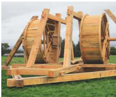
12 The ladder frame's main function is to support the two A-frames
