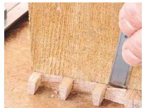
15 Remove any waste with a coping saw as before. Pare back to the shoulder line with a bevel-edge chisel
