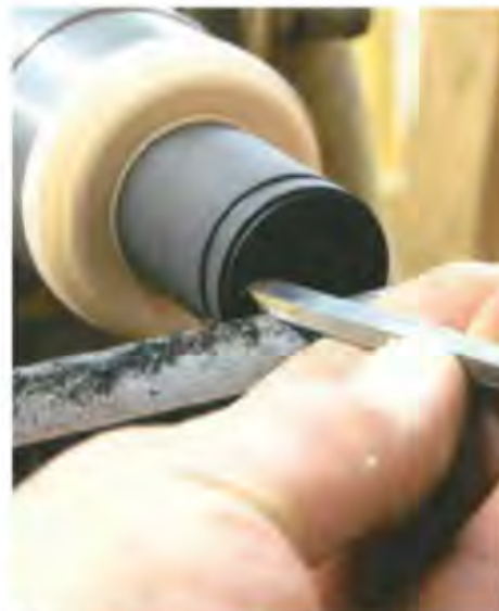
2 A 6mm scraper gives quick results when turning the concave
