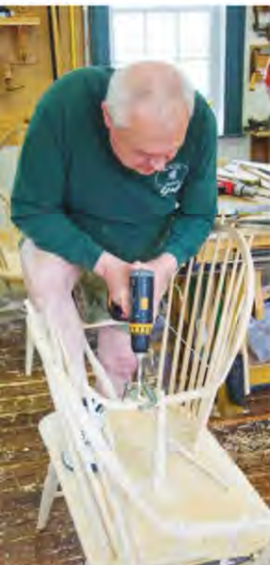
Mike drills a spindle hole in the arm of a tête-à-tête
