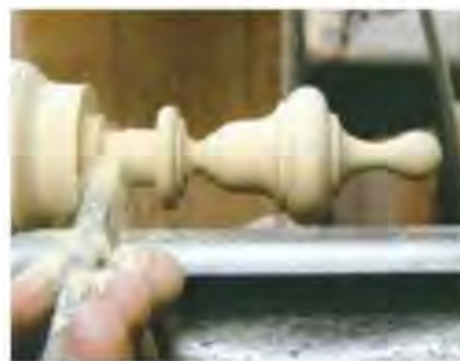
3 Turn the spigot with the parting tool and check it using Vernier callipers
