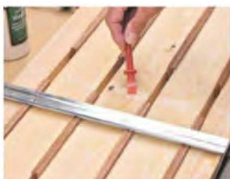
5 Keeping timber cramped, spread exterior PVA glue between the pencil lines previously marked
