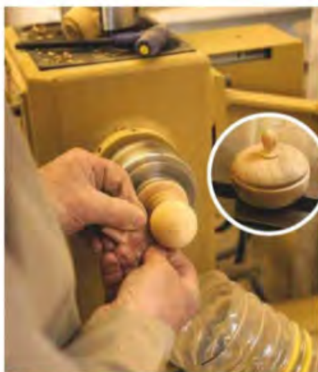
26 I hand sanded through the grits from 80 to 240 and then fitted the egg to the top of the lid
