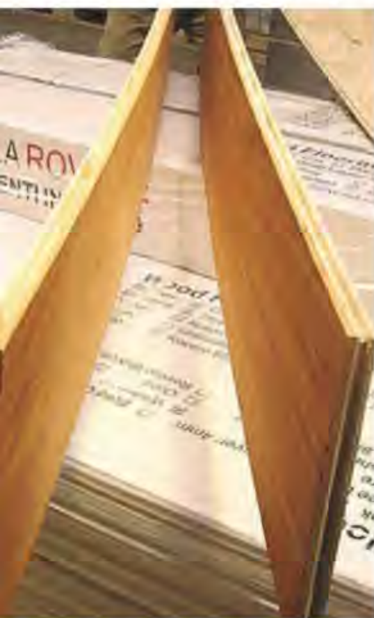
Bowed engineered wood flooring
