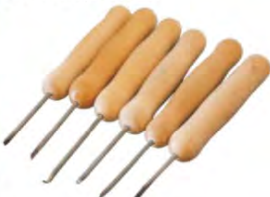
5 My home-made mini tools are just sharpened up masonry nails that protrude around 65mm
