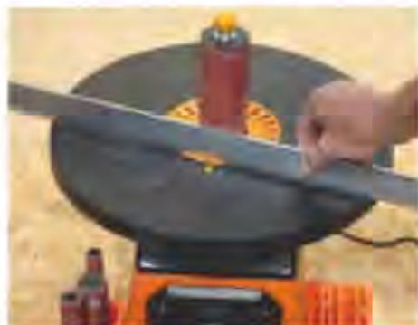
I found the work table was not completely flat when examined with a straightedge, a common problem with aluminium tables
