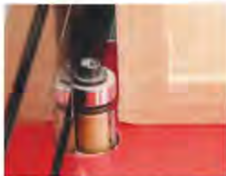
7 A bearing-guided trimming cutter makes short work of trimming round the box
