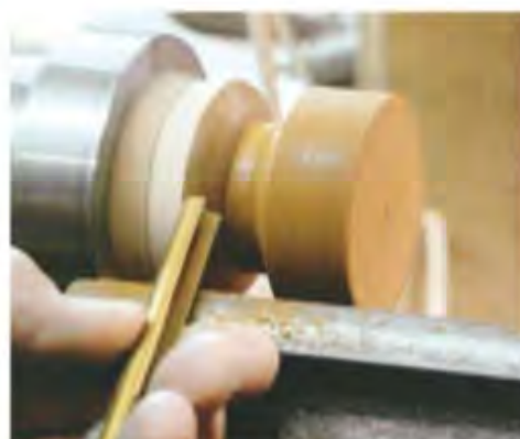
1 Starting with the back plate, turn the knob to the finished diameter...
