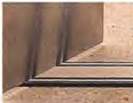
9 Clean chisels make judging mitres much easier by viewing the cut at a 90° angle in the reflection on the chisel
