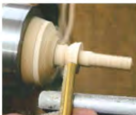
4 Once threaded, use the 6mm gouge to round over the end of the spigot
