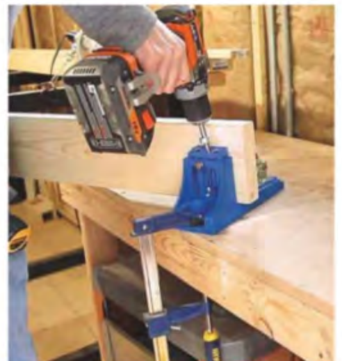
5 Using the Kreg Jig to drill pocket holes
