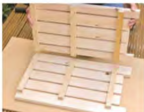
8 Build the remaining two side panels with shorter battens; make sure adjoining sections fit together snugly
