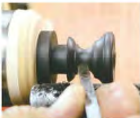
5 ... and a freshly sharpened 6mm scraper to turn the concave
