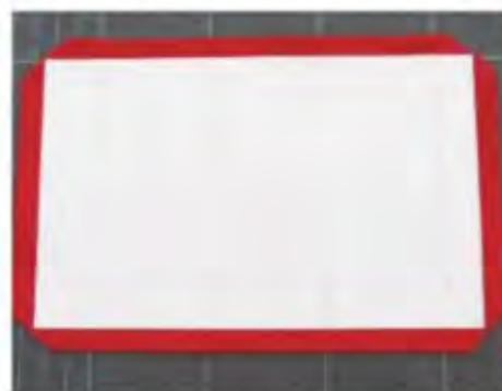
18 The bottom panel lining ready for the edges to be folded over and applied to the box
