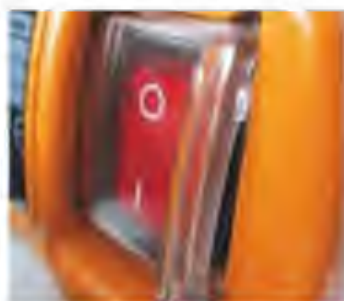
On/off switch is positioned behind a shutter to prevent accidental starts
