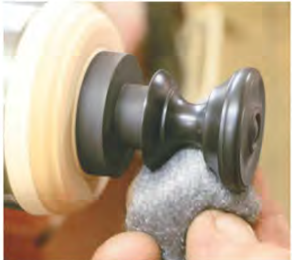
6 After sanding, use '0000' wire wool for the final finish
