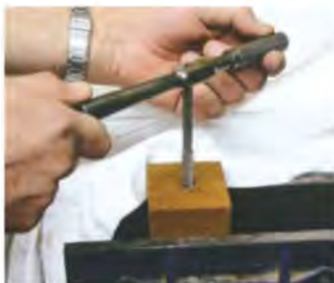
1 Cutting threads in face timber, is easy; just keep the tap square and work slowly
