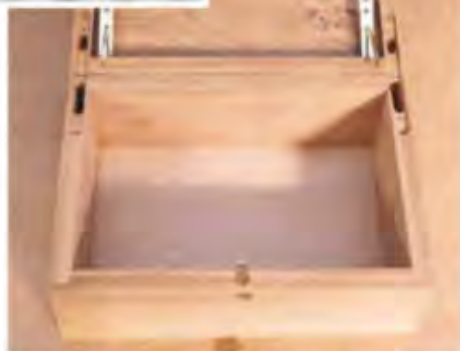
15 Hinge housings cut and pilot holes for screws drilled. The three holes required for fitting the button catch have also been drilled
