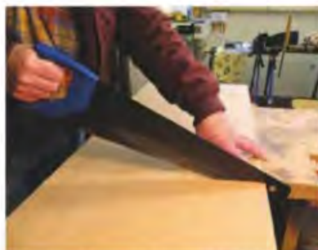
4 And cutting. You know how to cut to a pencil line for absolute accuracy, although not everyone does it quite the same. Please note that the piece nearest the camera is very well supported so that the last part of the cut will not break nor will the piece fall to the floor
