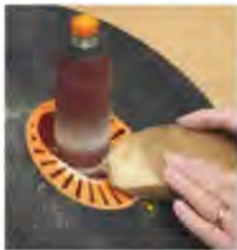
As with most sanders you'll need a cleaning block to de-clog them every so often and extend abrasive life
