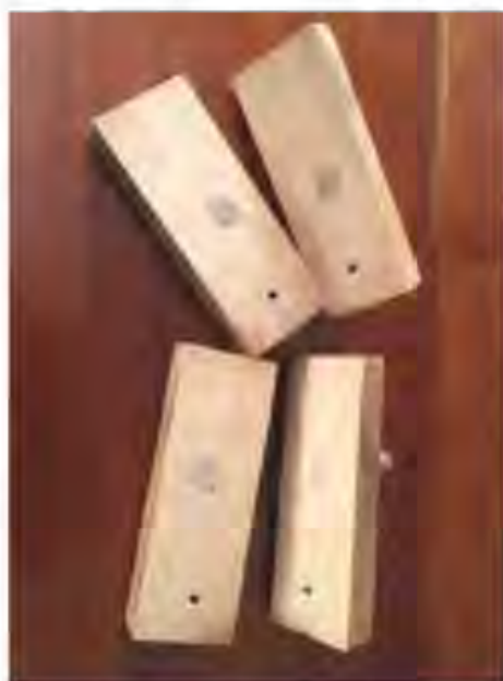
9 A pair of sample joints that I cut apart to show how the faceted oak tenon distorts a hole in a soft wood. I made these joints more than 30 years ago and they remain tight
