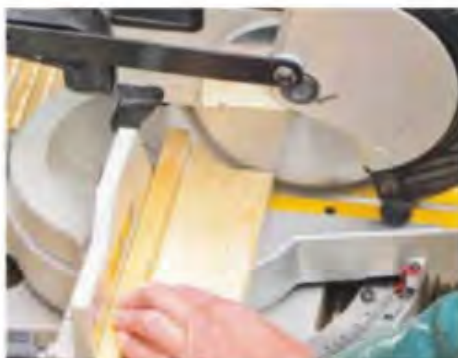
1 Cut softwood to length, checking that all 12 inner rails are 40mm shorter than the legs
