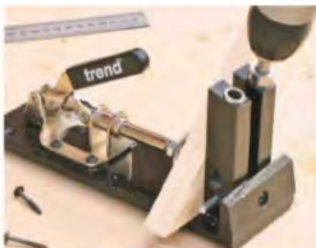
14 Use a pocket-hole jig for the mitre joints; experiment with drill depth and angle on offcuts first
