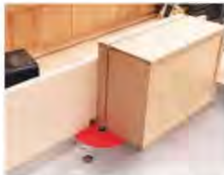
10 Using the original router cutter to complete the parting off of the box lid
