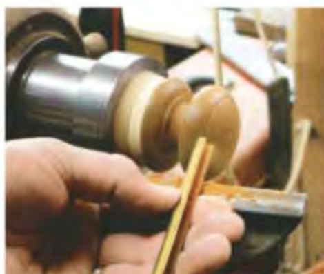
2 ... then round over the face with a 6mm gouge; keep the bevel rubbing to a good finish
