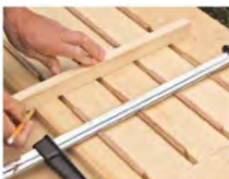
4 Lay the middle batten across the rails and mark to length. You need to cut six pieces at this length
