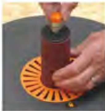
... while a sturdy clamping knob is used to tighten each one firmly on the steel spindle
