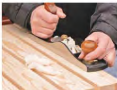
11 When the glue has dried, trim the edges of the legs flush with a bench plane. Lightly chamfer corners and remove arrises
