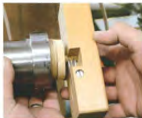
2 Separating the block to cut more thread before coming up against the shoulder
