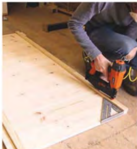
3 Using the finish nailer to assemble the headboard
