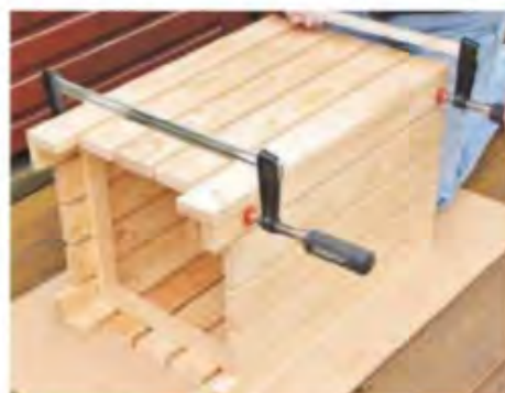
9 Apply glue to edges and cramp the panels together. Check ends for alignment and square
