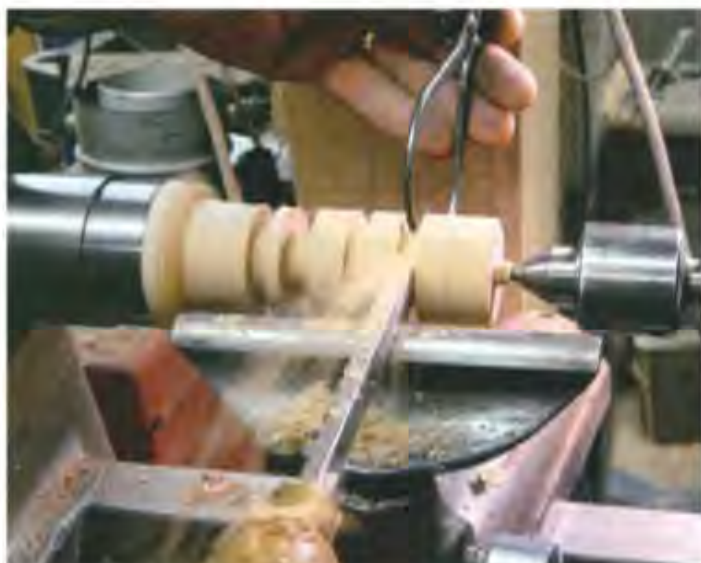
1 Two-handed: turn the fillets until the callipers indicate you've reached the correct depth
