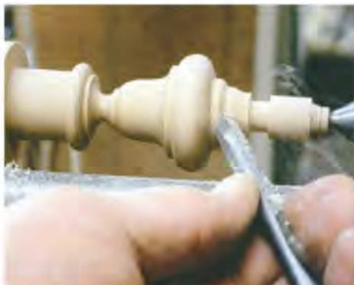
2 Use the detail gouge to turn the rest of the finial; keep your work crisp and sharp
