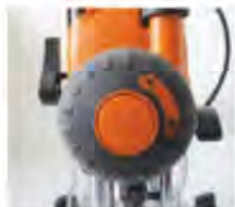
With the button out, plunge is locked
