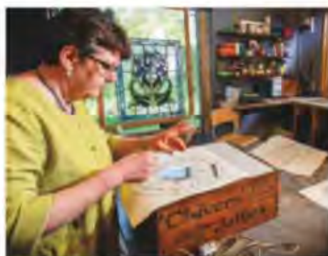
Applying a resist to glass prior to sand-blasting – the safer alternative to acid-etching
