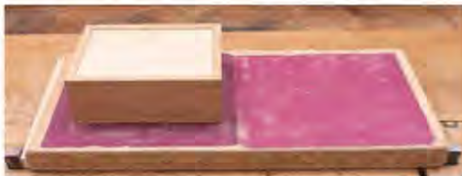
11 Abrasive glued to a flat board is used to remove feathering left by parting off the lid
