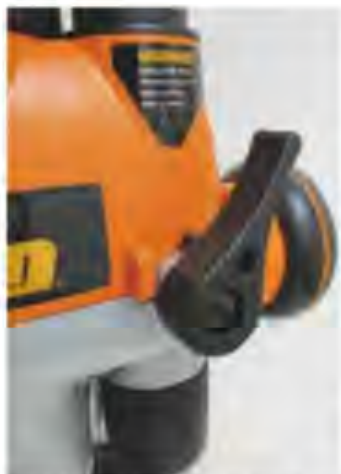
The plunge lock lever is well placed
