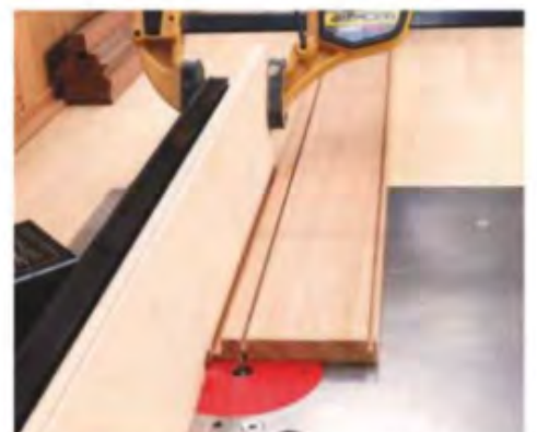
1 Rebate (L) is for lid panel and groove (R) for bottom. The two adjacent grooves are where the lid will be parted off after assembly
