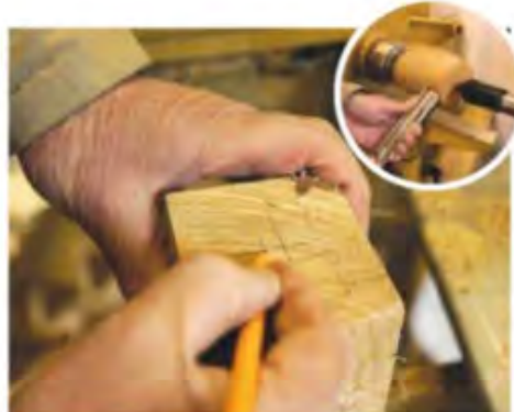
24 To do this, I started with a square piece of stock and turned it from square to round using a spindle roughing gouge
