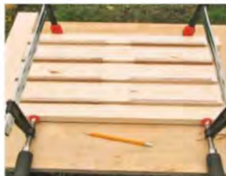
3 With 12mm plywood spacers between them, cramp together legs and rails. Any defects should be face up
