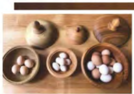
25 I turned a spigot using the beading/parting tool and shaped the finial into an egg shape using a 10mm spindle or bowl gouge – this is probably the most used tool in my turning arsenal
