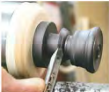
4 Use the 6mm detail gouge to shape the rest of the knob...
