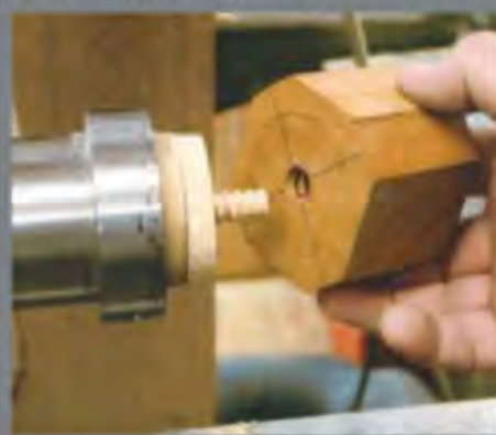
Screw the timber onto the thread; don't over-tighten it or you'll break the thread
