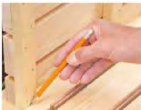
7 Once you've made the first pair of side panels, mark against the adjoining legs. Cut six more battens to length
