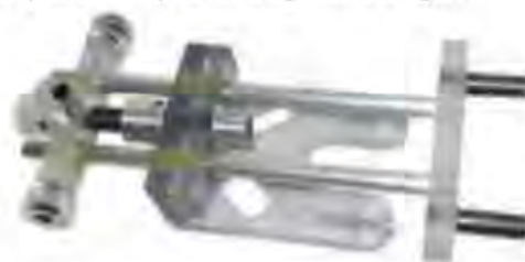
Colin's homemade Perspex version of the Micro Fence – Edge Guide, which was recently tested by Phil Davy in the February 2019 Issue
