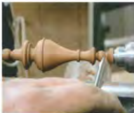
4 A Steb centre and revolving cup are ideal for split turning. Turn the balls on the ends last
