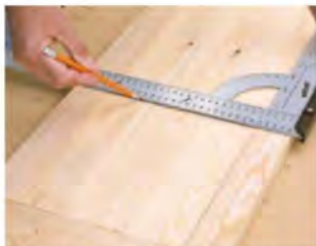
2 Butt ends of two narrow legs and three rails against the timber and mark lines across for the horizontal battens
