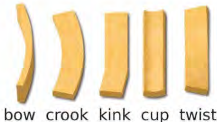
Diagram showing wood warping
