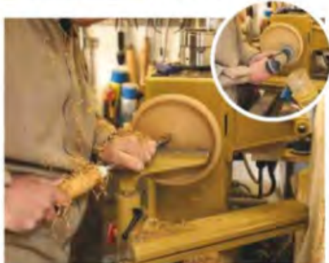
22 I could then turn and sand the inside of the lid as before
