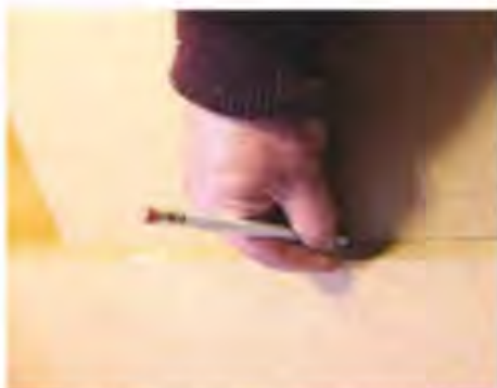
3 Marking the height of one side. I have both pieces resting on the MDF floor and vertical so that I can mark the height absolutely accurately
