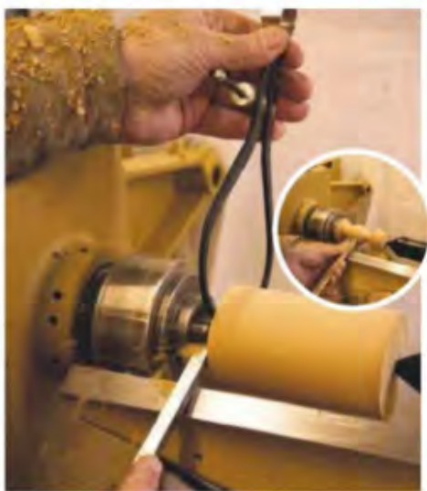
25 I turned a spigot using the beading/parting tool and shaped the finial into an egg shape using a 10mm spindle or bowl gouge – this is probably the most used tool in my turning arsenal
