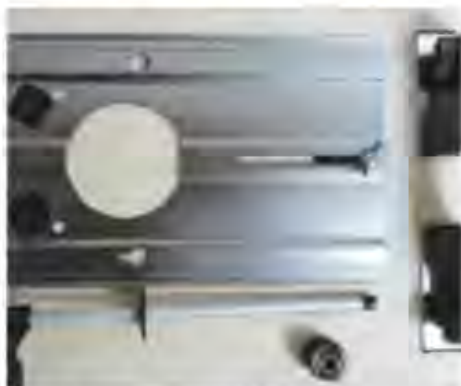
Supplied components, including a collet for 8mm cutters
