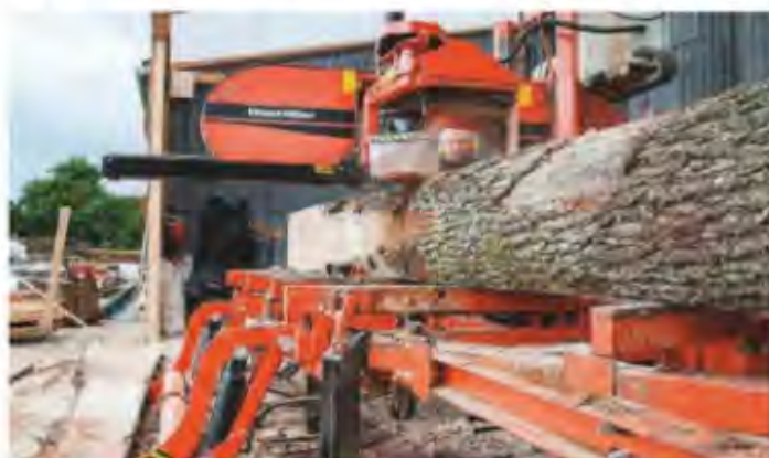
Sawing logs into finished lumber with a basic 'portable' sawmill
