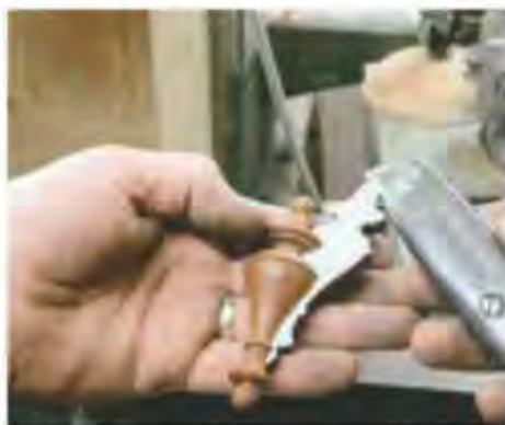
5 Identical twins: use a Stanley knife to split the finial in half
