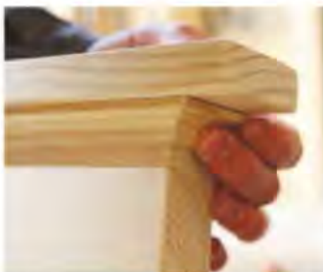
8 Cove moulding that was installed under the top cap
