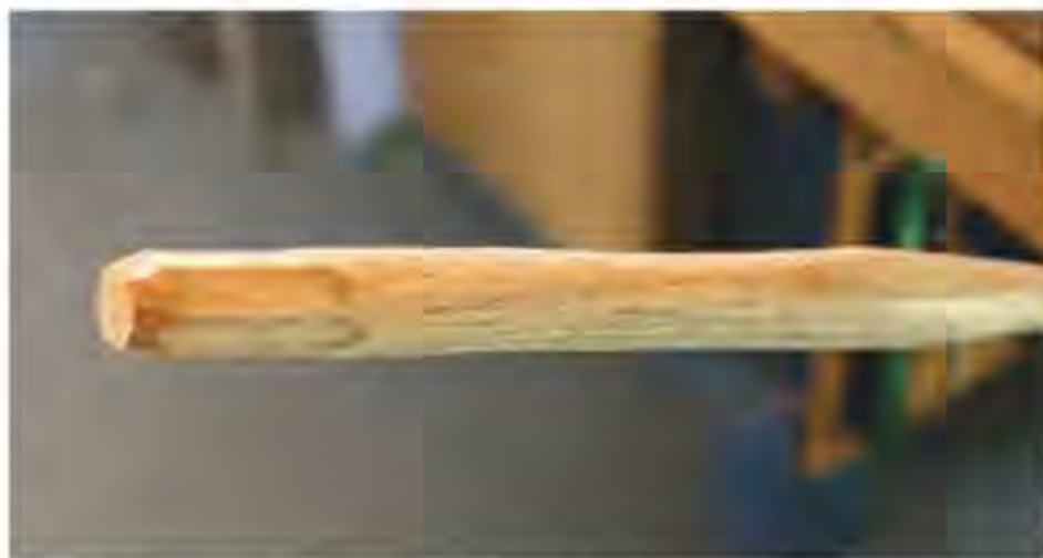
8 A slightly oversized faceted tenon on the end of a long spindle is driven into its hole in the seat with a hammer. Because the seat is made of a softer wood than the oak spindle, the hole distorts, conforming to the tenon's irregular shape. This joint is nearly impossible to separate
