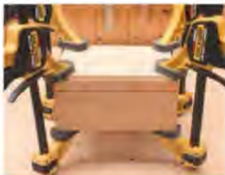
6 An MDF pressure plate, slightly smaller than the lid panel, spreads the clamping force. Take care to remove any glue squeeze-out immediately
