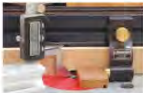
13 Router table set up for cutting the upper left and lower right hinge mortises. Use an accurately made hardwood spacer to set the length of cut and a height gauge to set the depth. The spacer and stop will be set to the left of the cutter for the remaining two cuts
