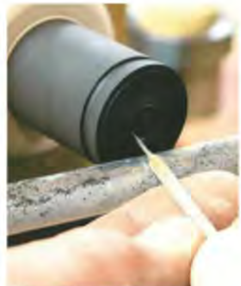
3 A home-made tool is used to apply the fine score line
