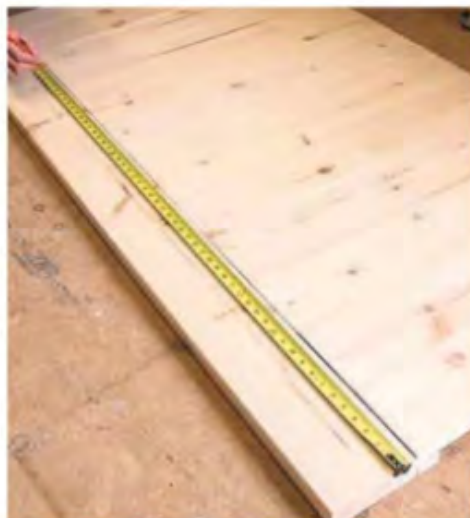
4 Marking where the pocket holes will be drilled
