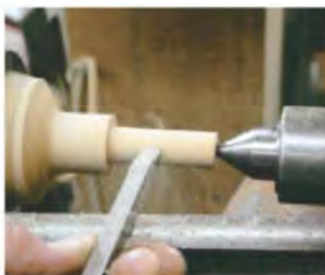
3 The spigot blank is mounted onto a screw chuck and turned to the finished diameter
