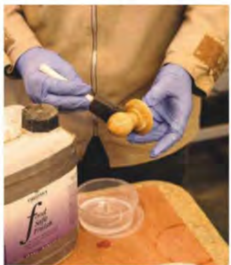
27 I used two coats of Chestnut Products food-safe finish on the egg bowl, allowing 24 hours between each coat, which I applied with a sponge applicator
