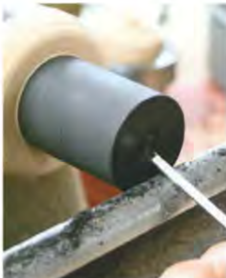
1 Turn the half-ball in the middle with a 3mm parting tool
