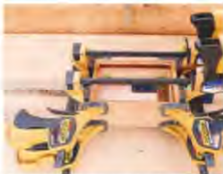
5 A pair of sash cramps provides a stable platform during the clamping. Soft-faced cramps provide good pressure without marking the timber
