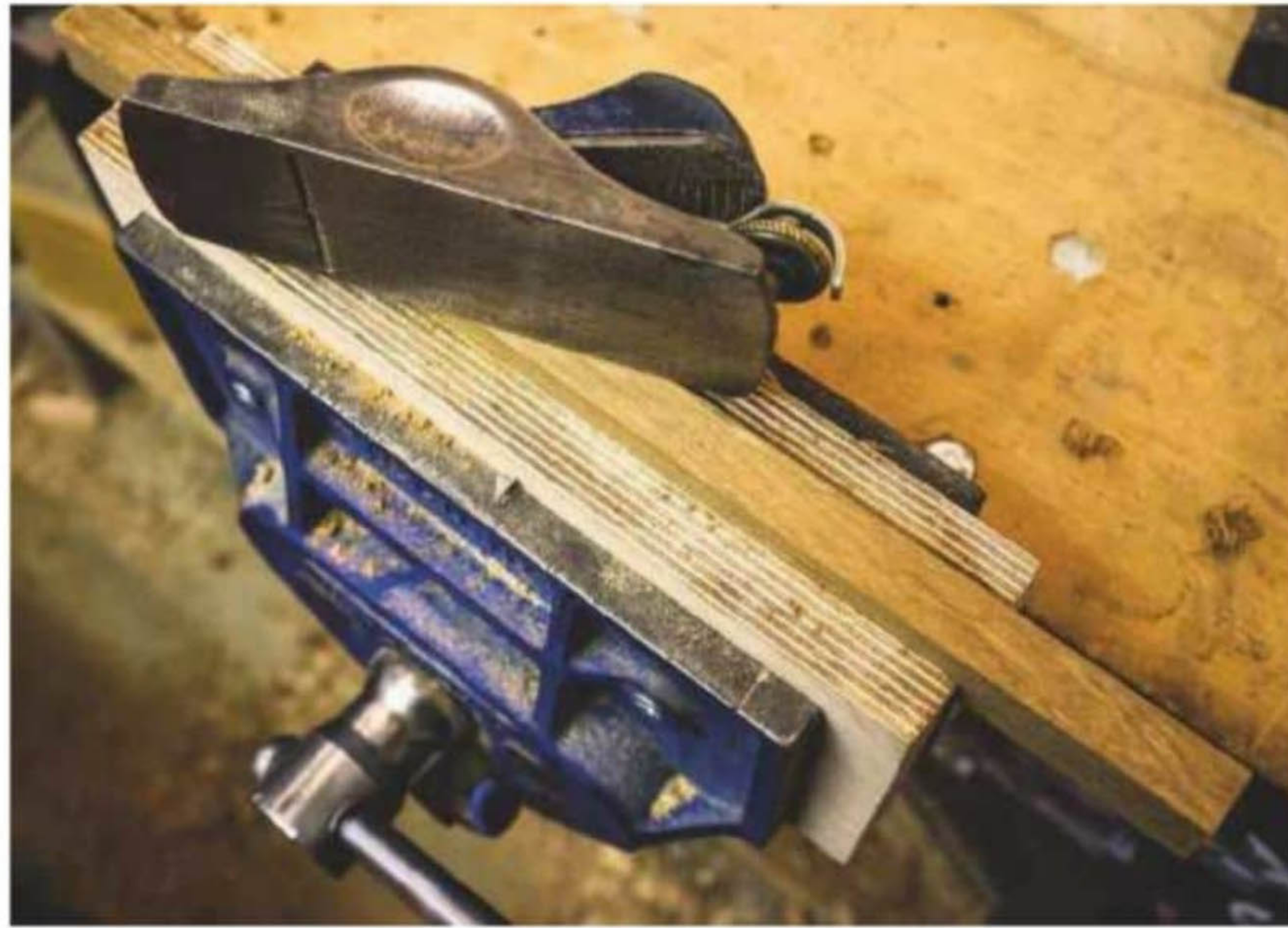
6 The shaft is planed to fit the hole in the body
