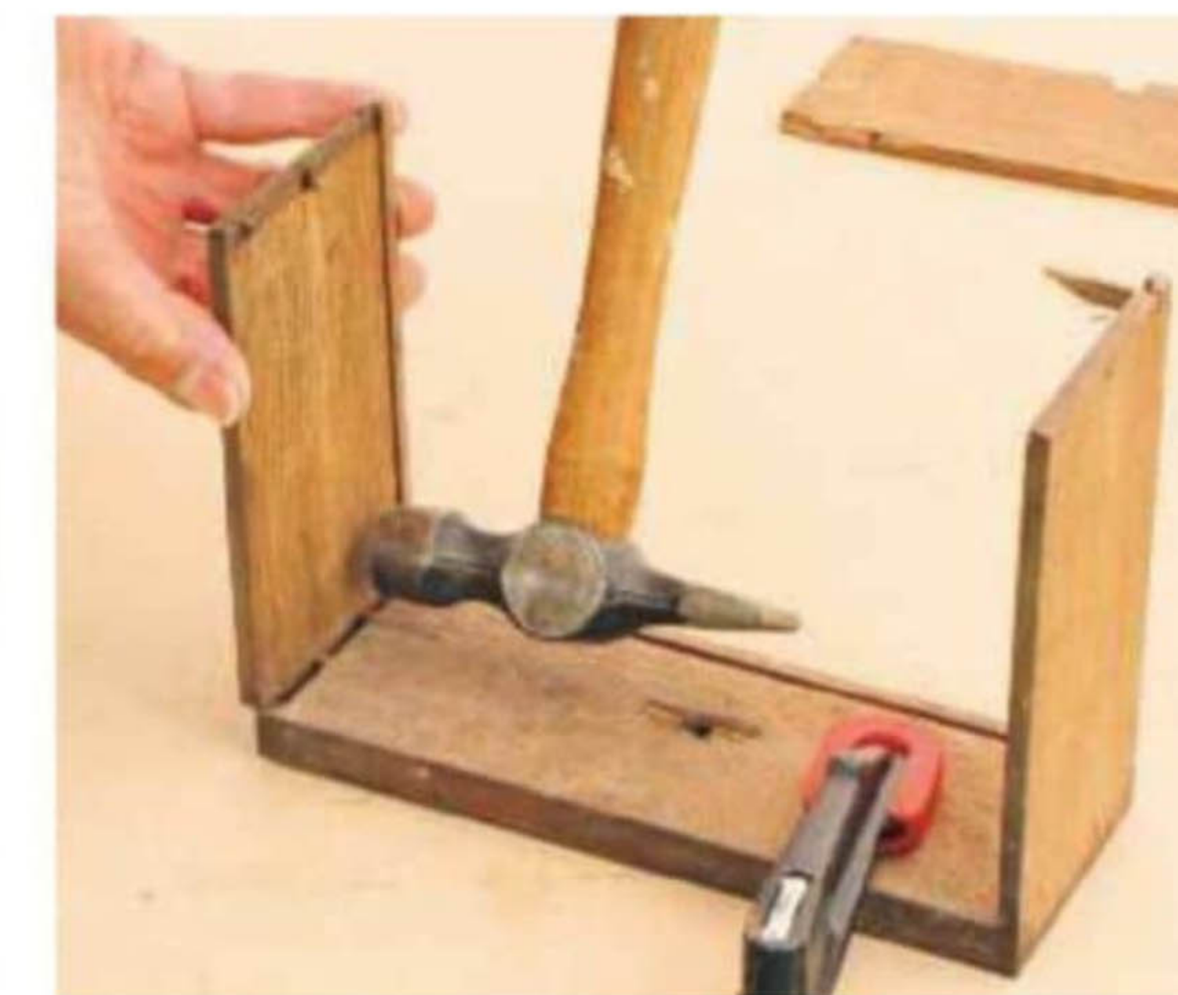
17 Carefully dismantle the drawer, tapping both sides gently outwards with a hammer or mallet
