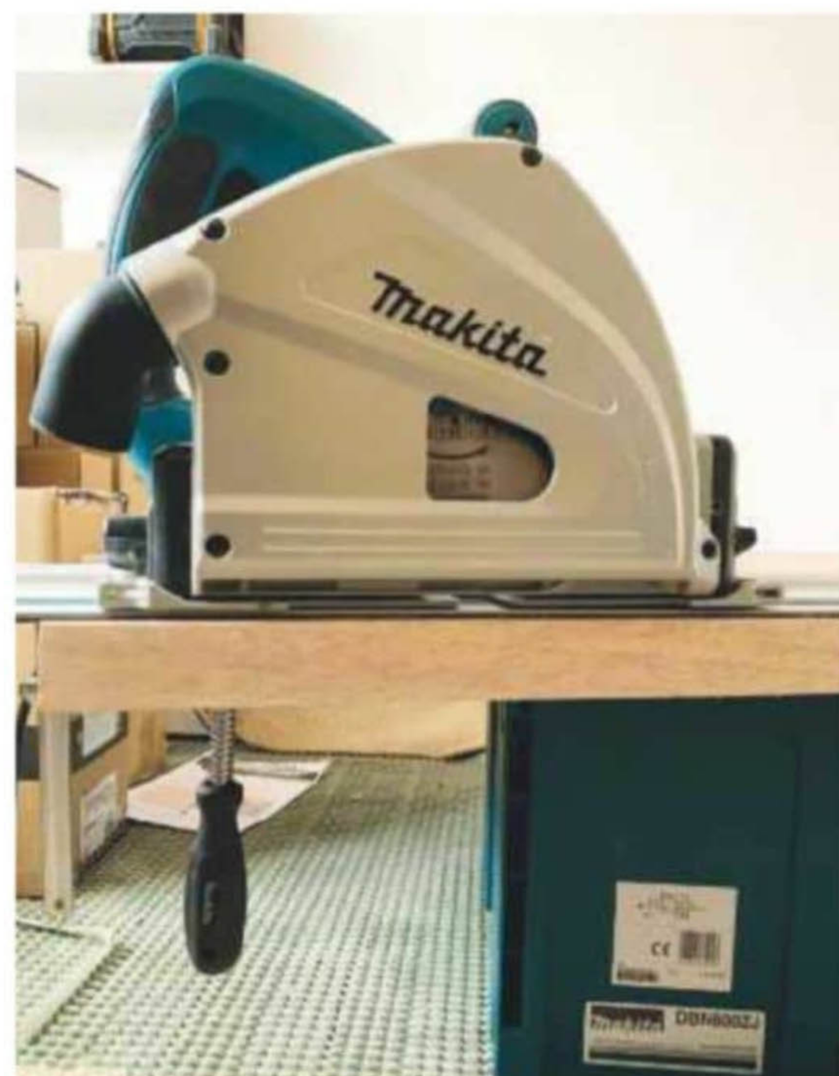
Track clamped in position and saw ready to cut
