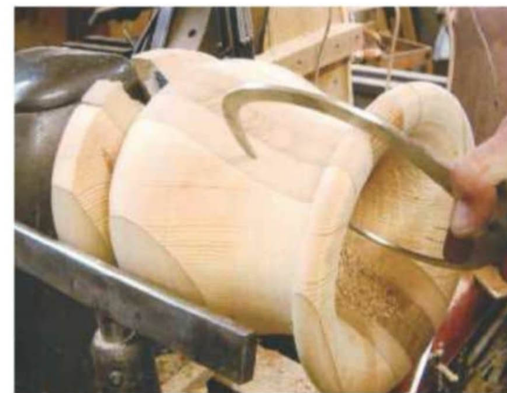
6 Stop the lathe occasionally and use figure-of-eight callipers to check the wall thickness
