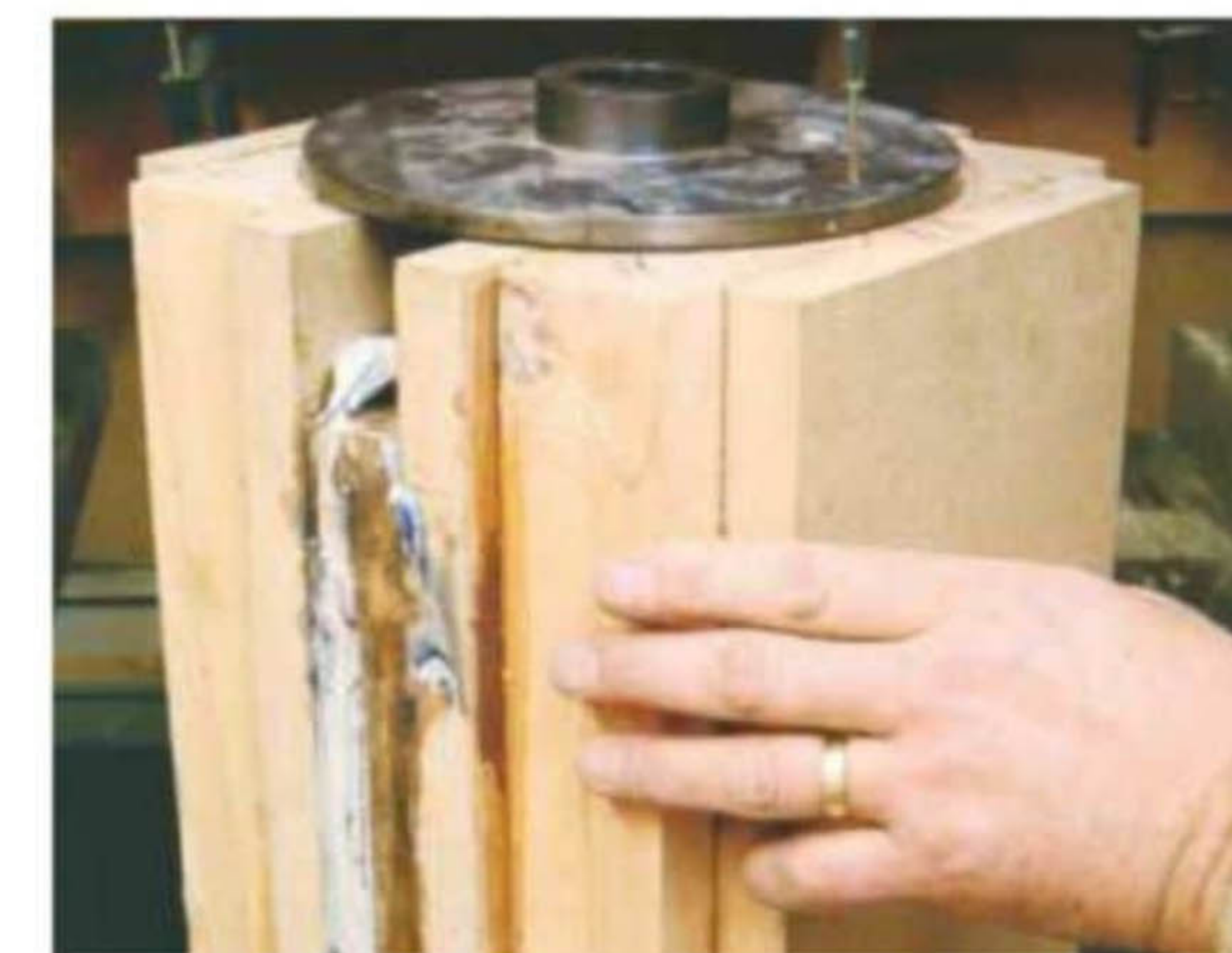
2 Screw a large faceplate to the blank using plenty of screws
