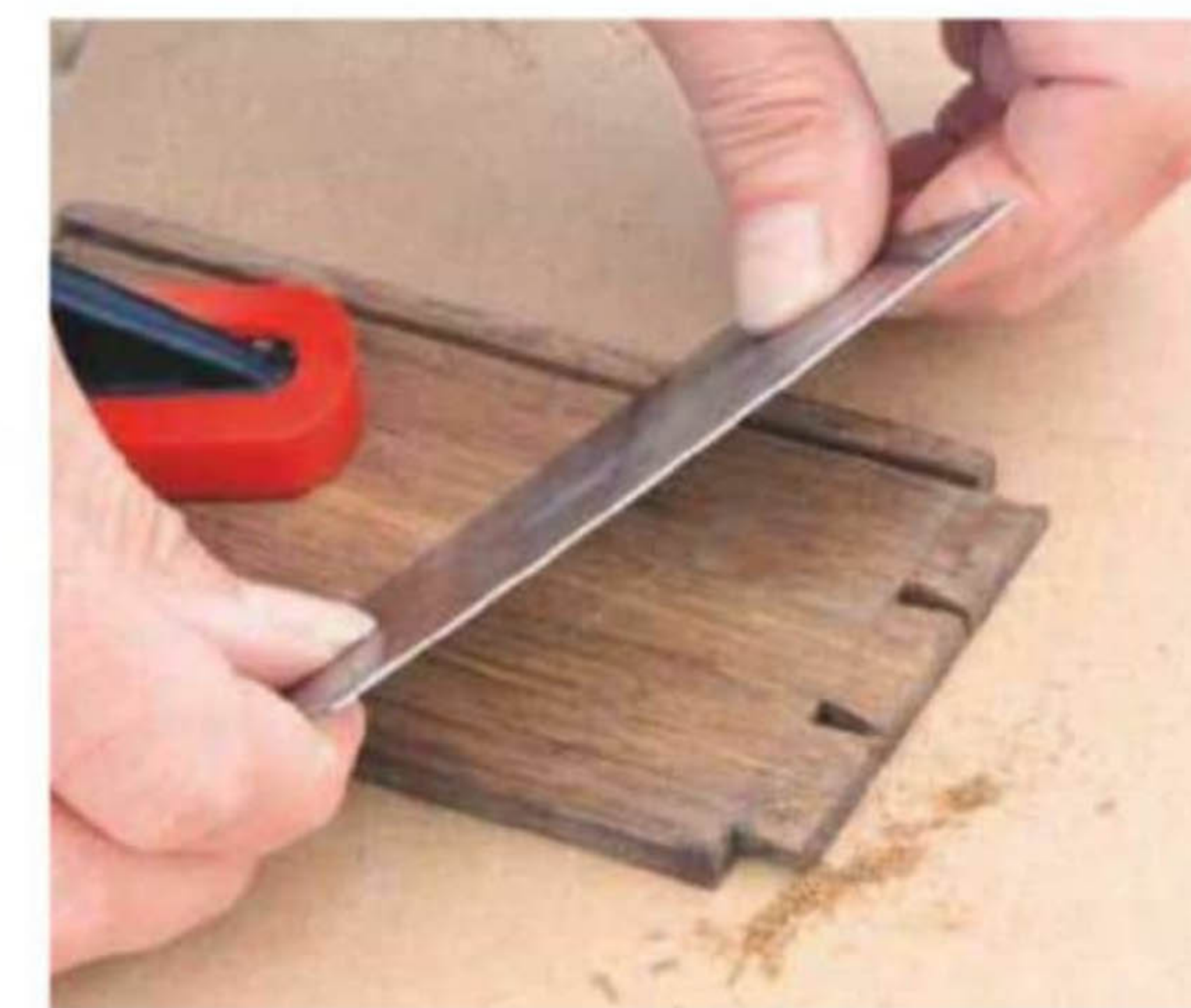
19 With parts disassembled, clean up inside surfaces of the drawer with a cabinet scraper
