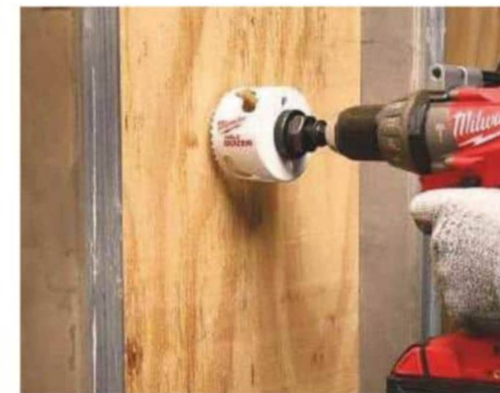
Using a hole saw to drill consistent holes in sheet material
