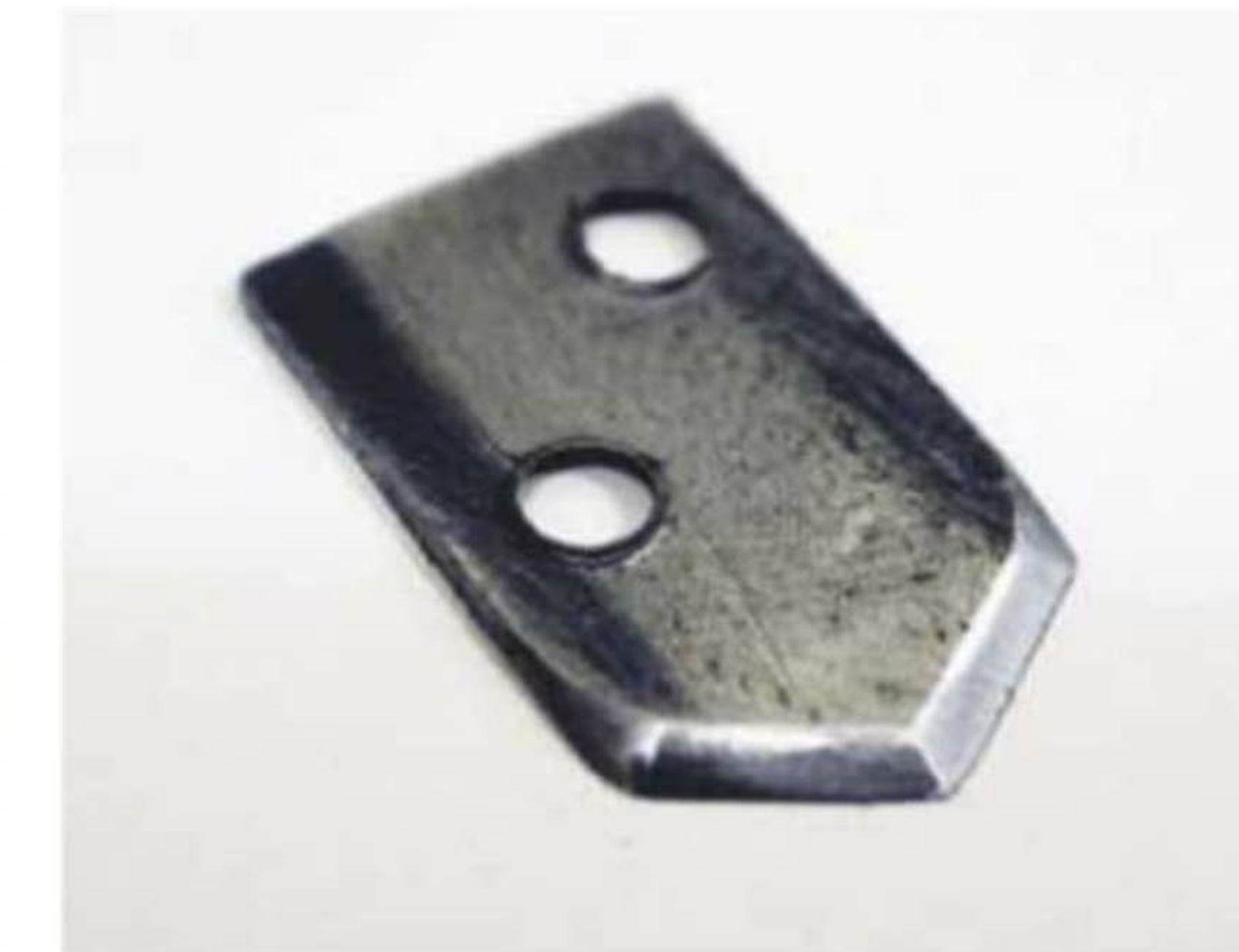
16 The blade is a little piece of tool-steel filed to an appropriate shape and sharpened with a single bevel
