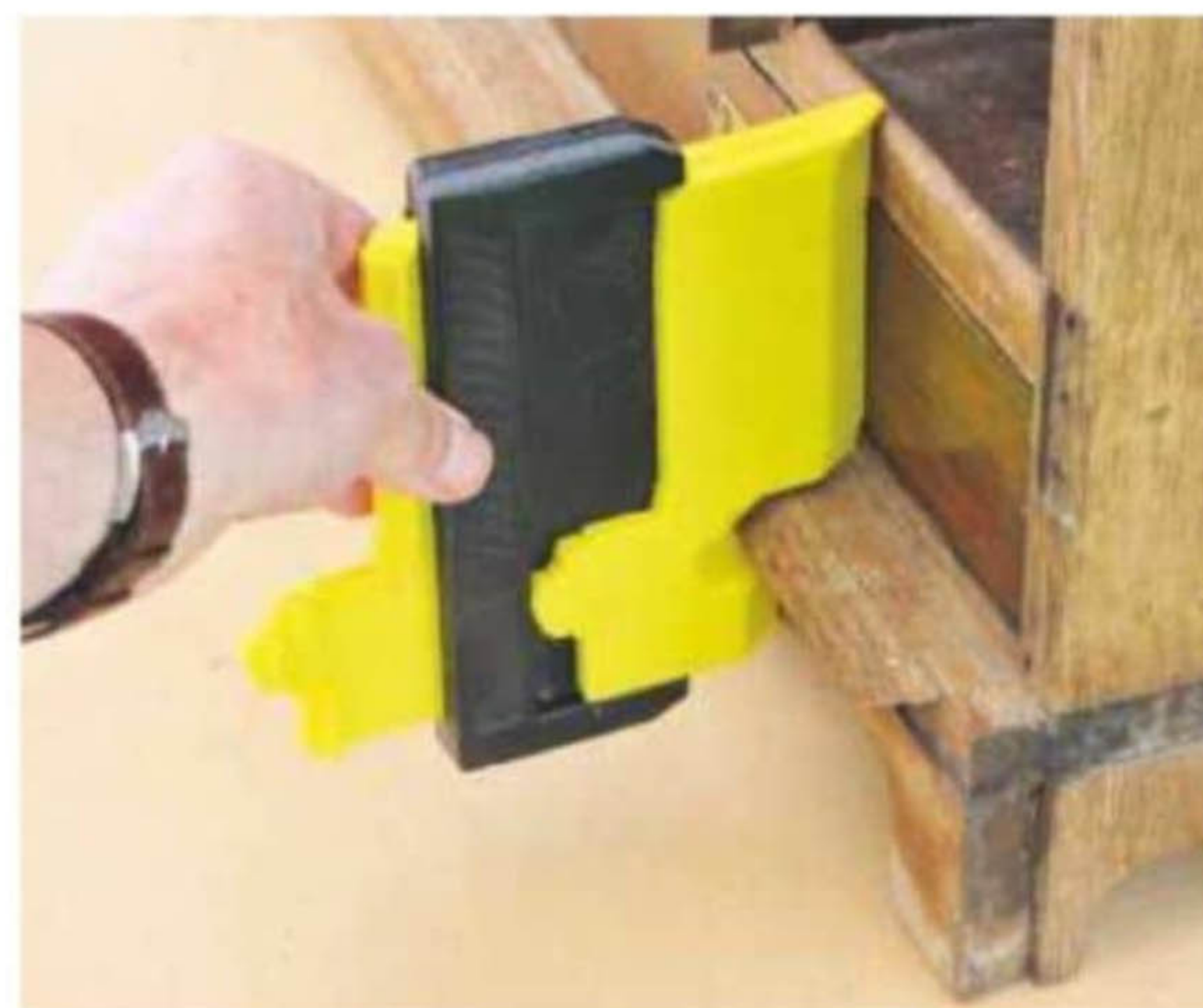
4 Using a profile gauge against the existing moulding will help get a perfect match on replacement
