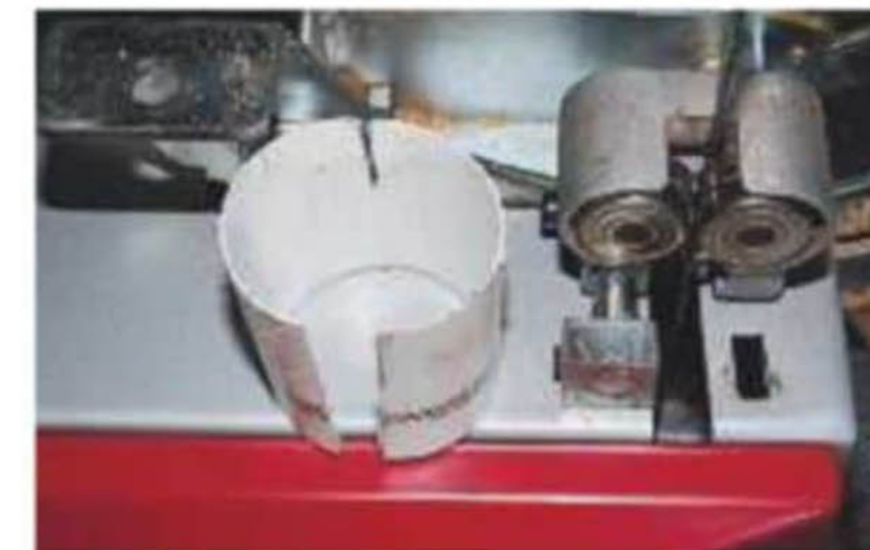
Plastic sleeve made from tube of used plastic sealant and lower guide bearing prior to fitting
