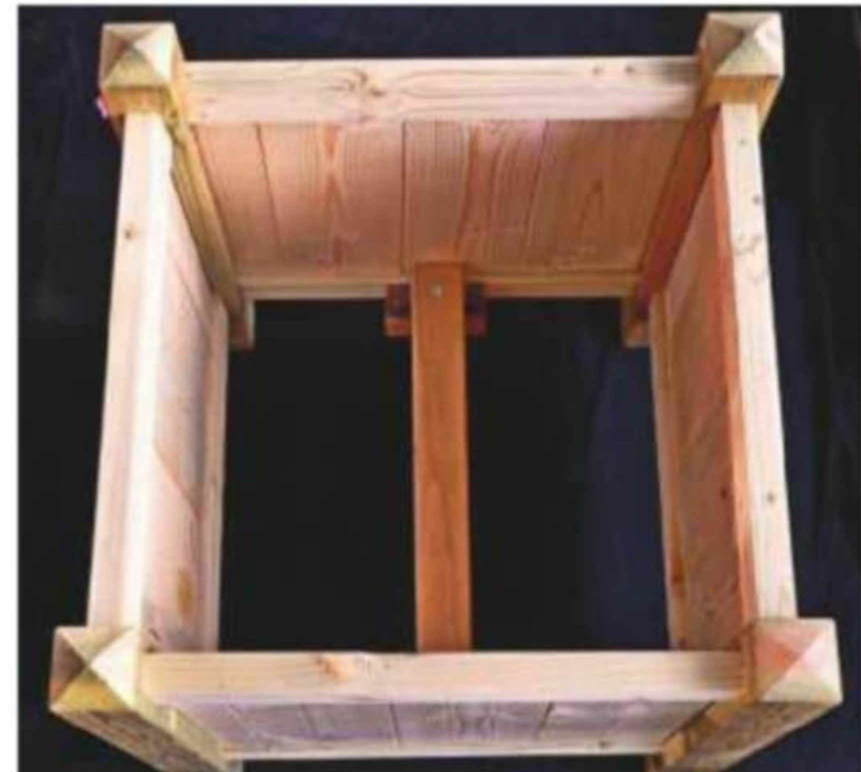
13 View from above, showing the tub-supporting batten and attachment blocks
