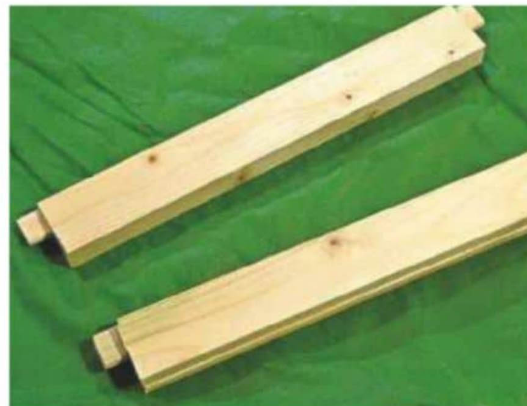
18 Oops – the embarrassing mistake – legs with mortises cut in the wrong place, and 'bastard rails' made to solve the problem. Showing a bastard rail with a correct one
