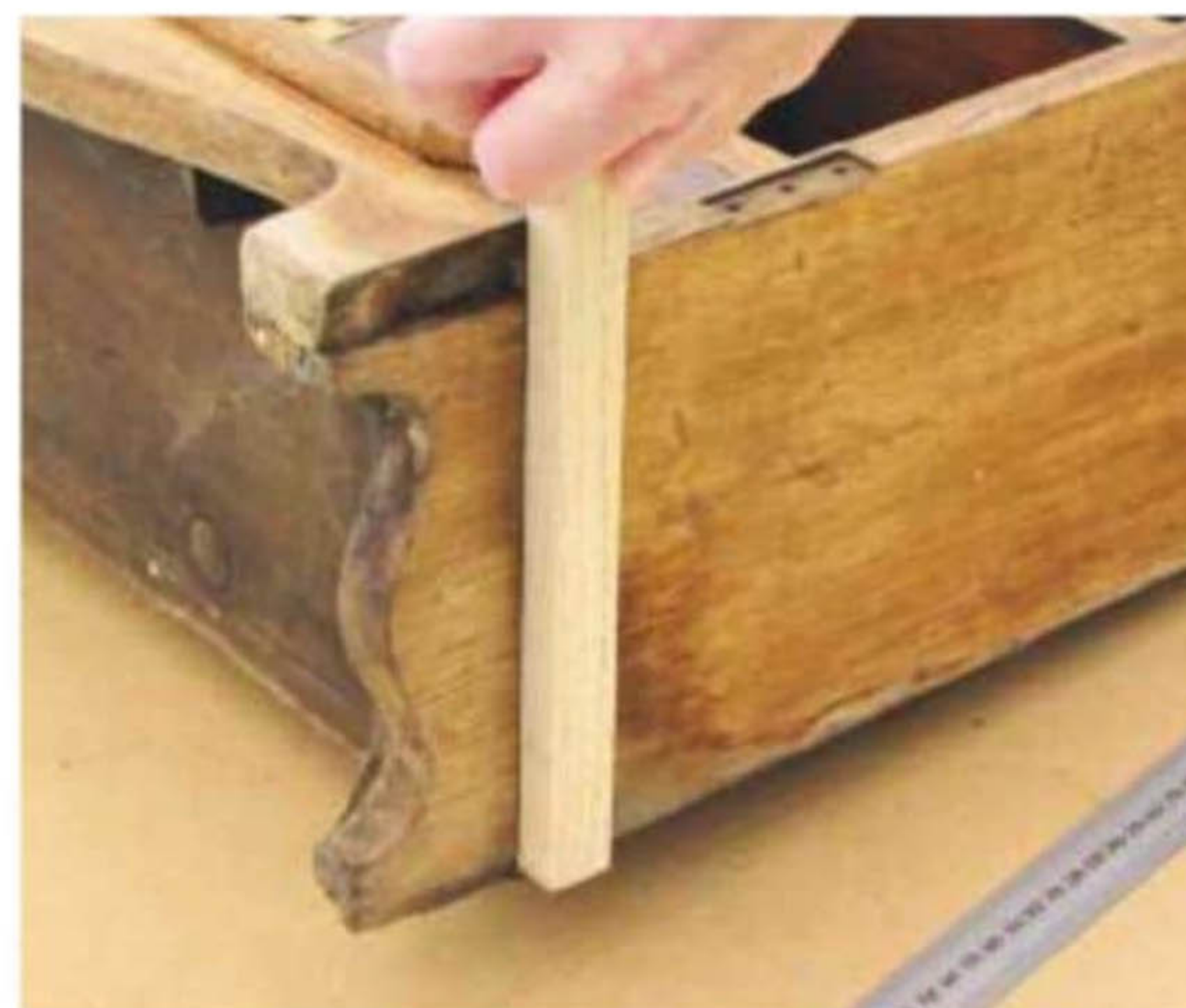
5 Plane new oak to size and check for a snug fit in the housing; shape before cutting to length
