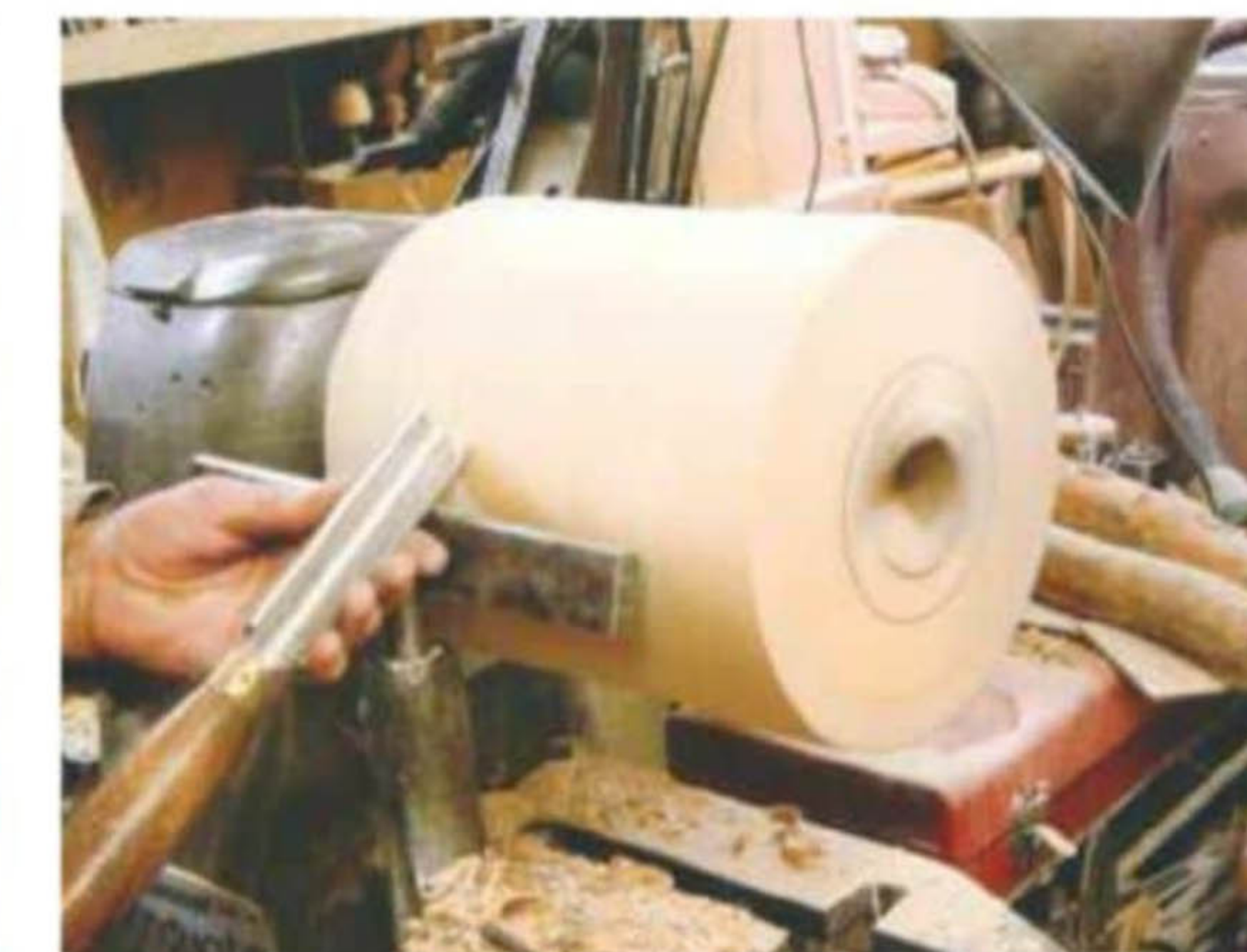
3 Mount the blank on the lathe and turn it to the finished diameter...
