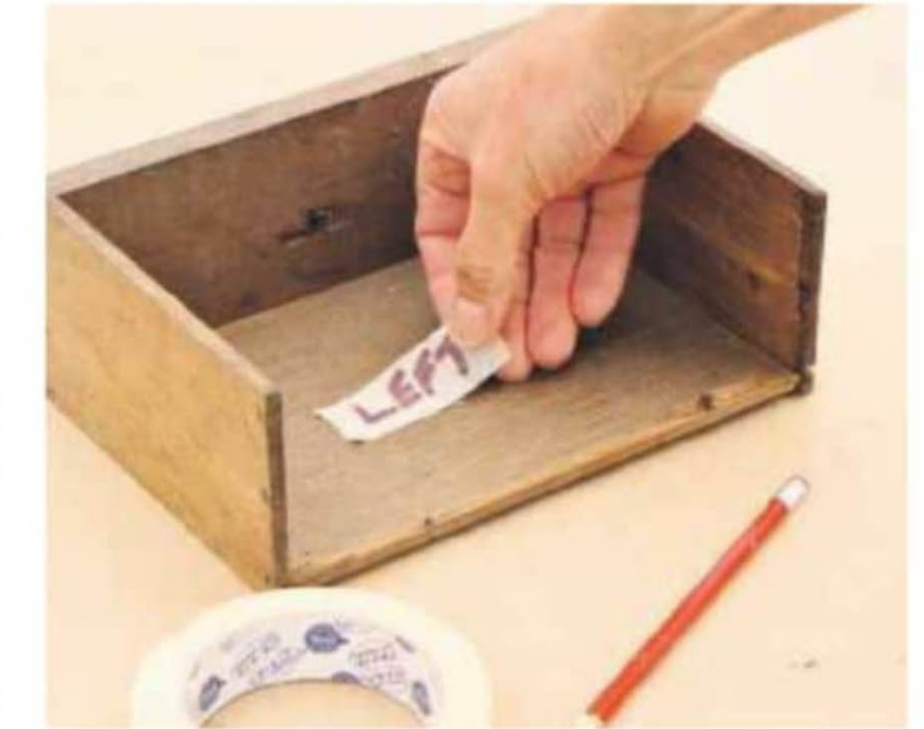
15 With almost identical drawers, it's wise to label with masking tape to prevent mix-ups
