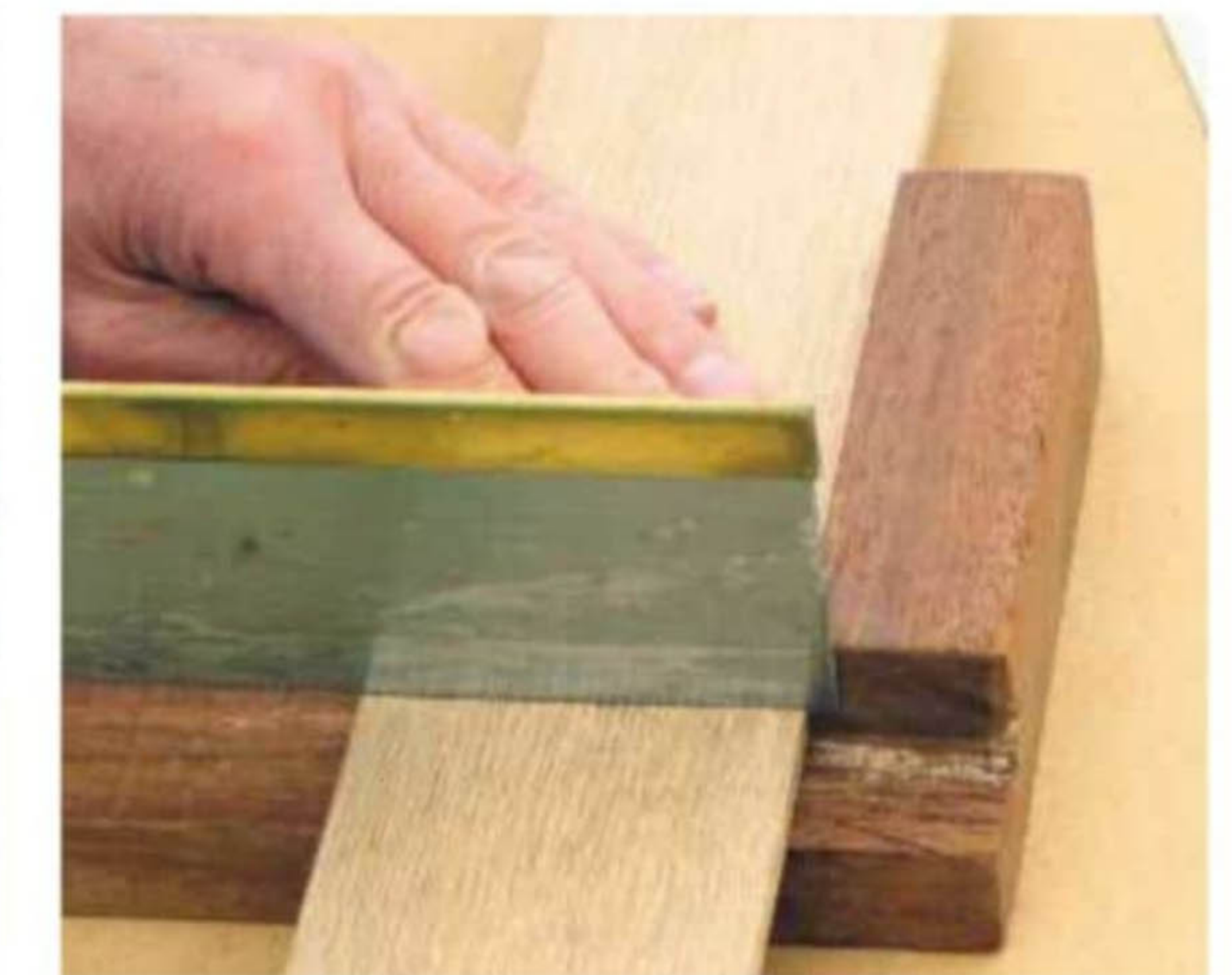
21 Measure the drawer front and cut replacement back about 2mm longer for trimming later
