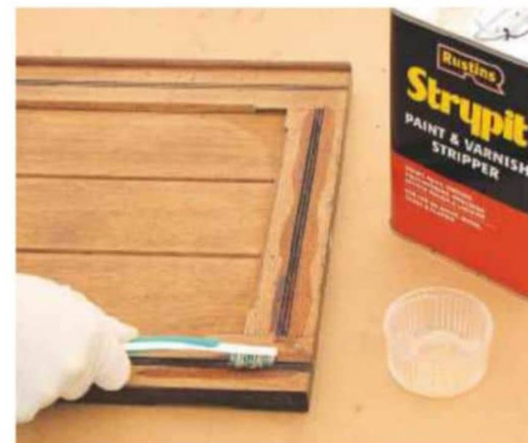
12 Remove old finish from reeding with Rustins Strypit applied with a discarded toothbrush
