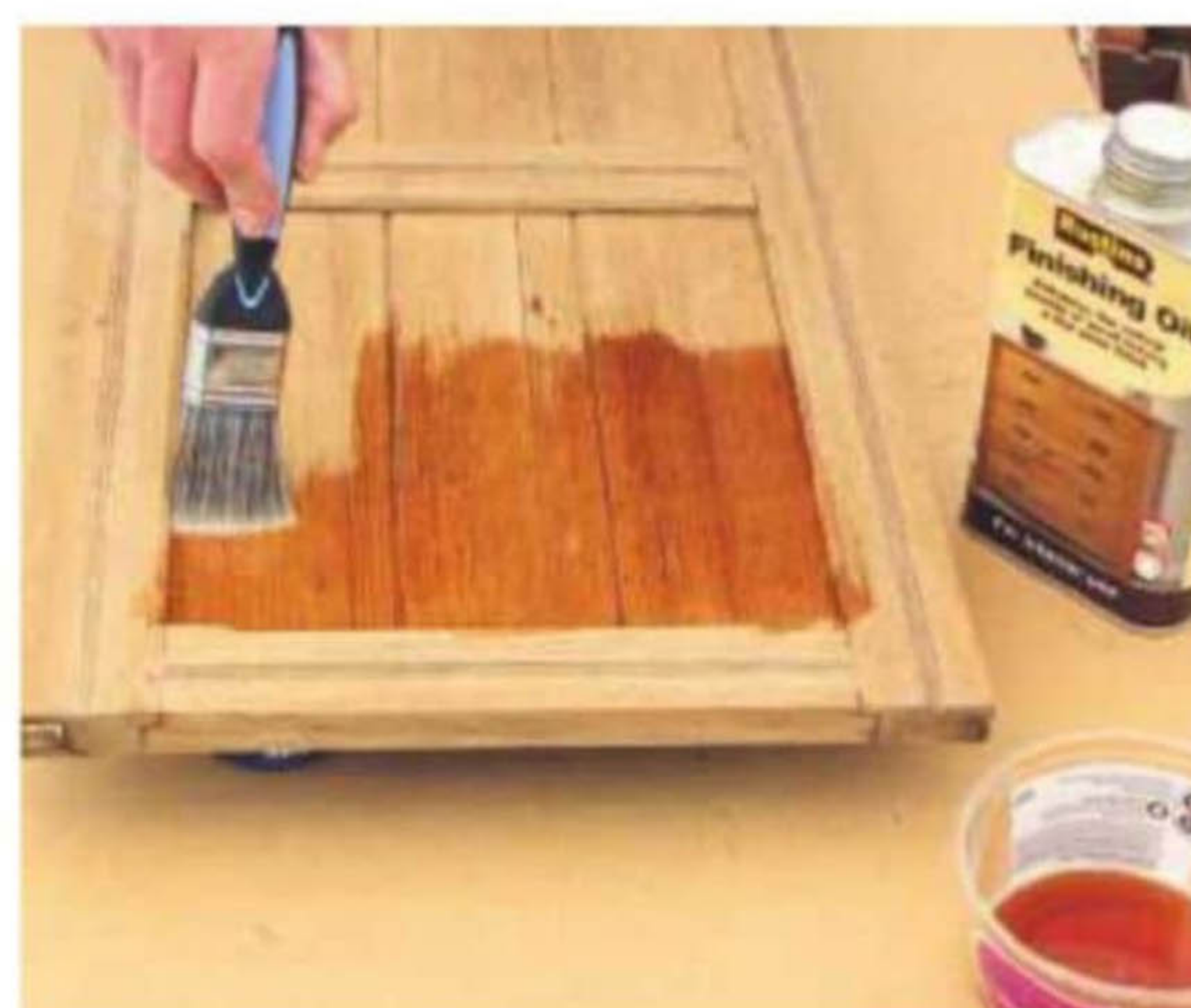
35 Dampen surfaces to raise the grain, then lightly sand; apply two coats of Rustins Finishing Oil
