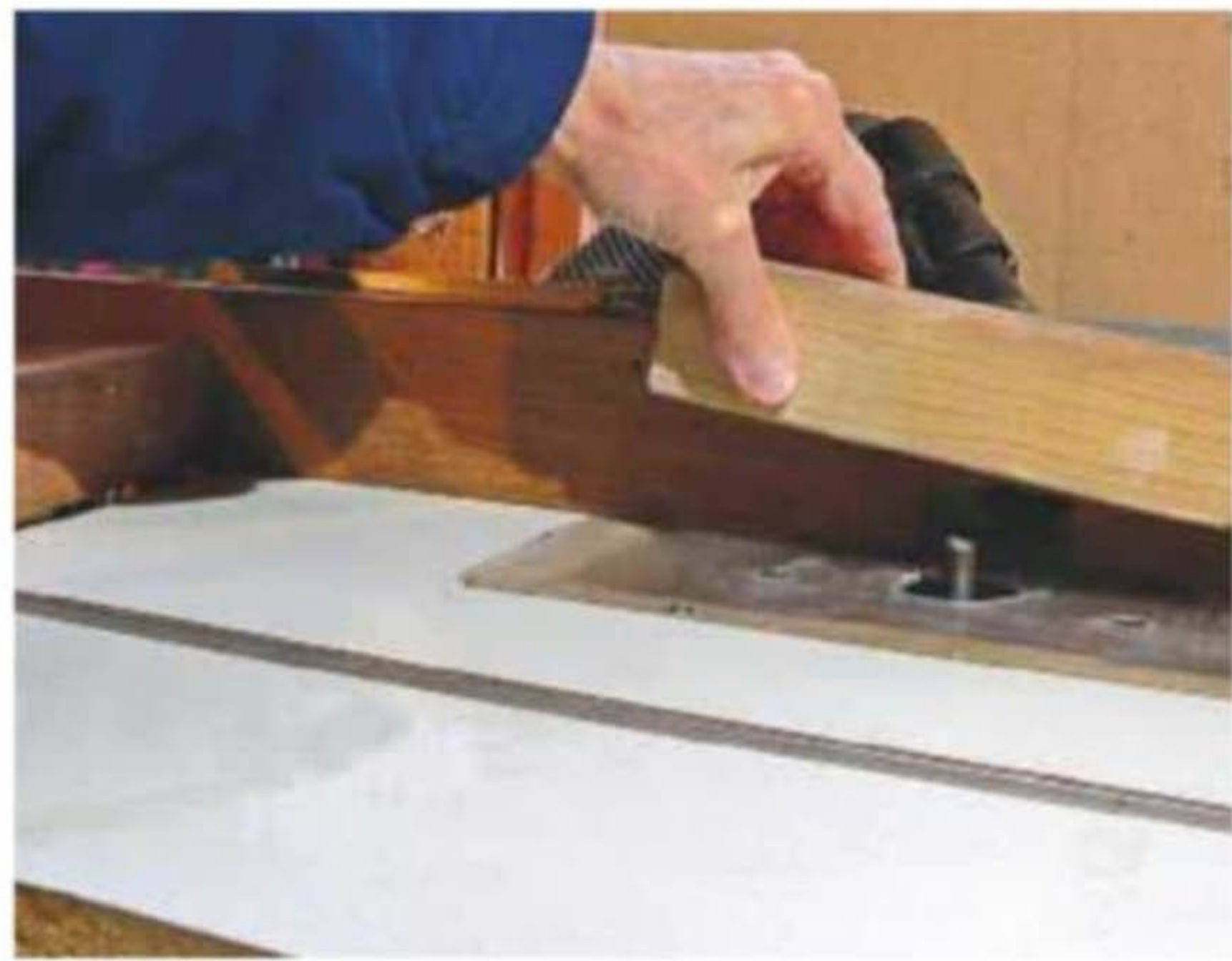
4 Dropping the leg onto the router cutter to make 10mm slots
