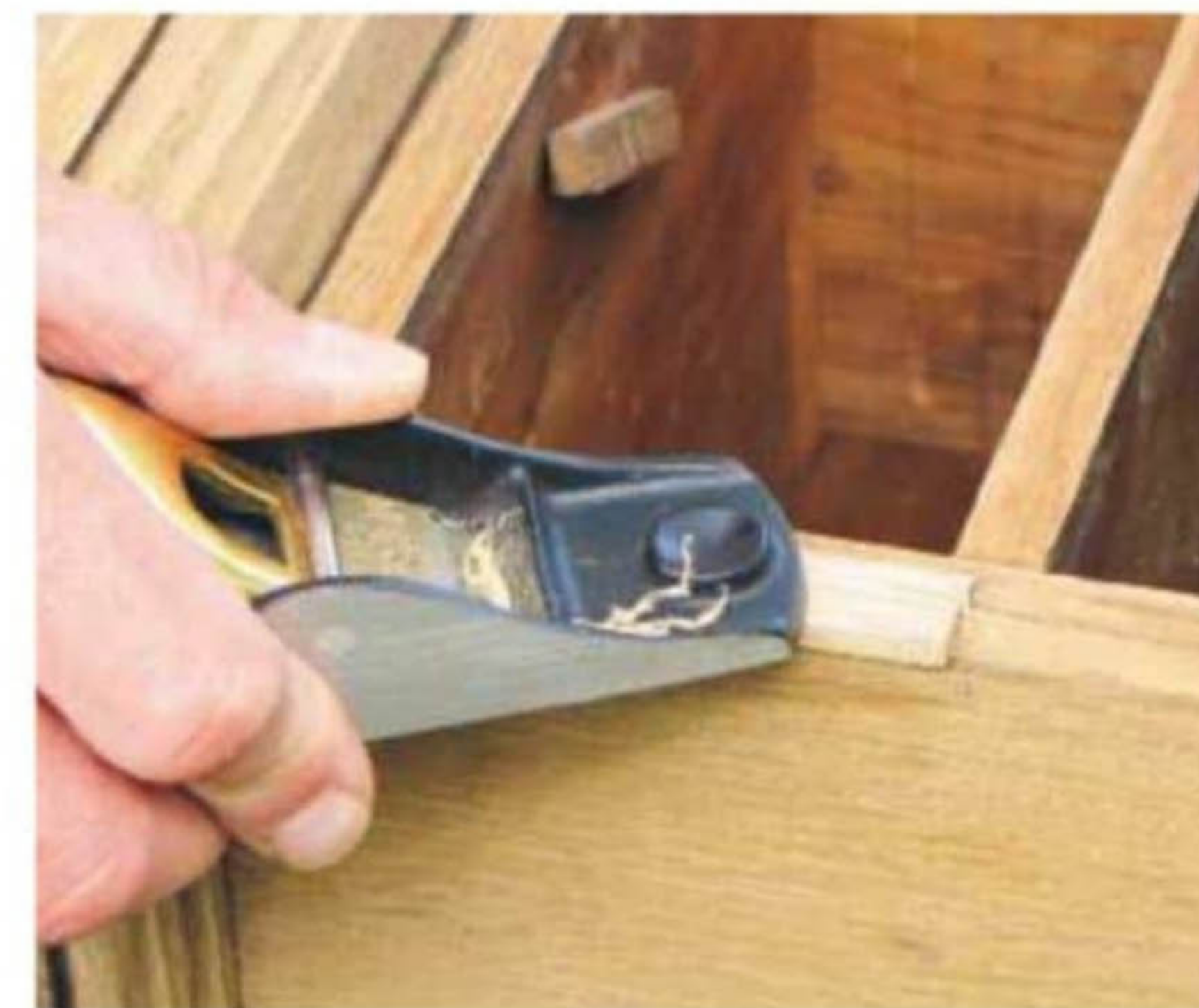
9 Remove excess with a fine-toothed saw and trim flush with a block plane; repeat on carcass
