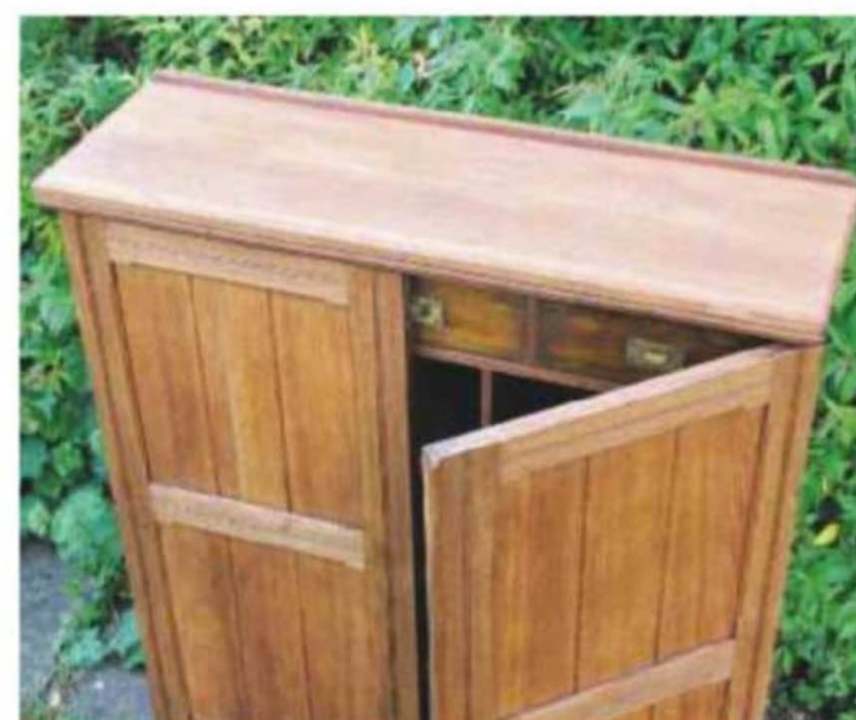
36 Adding a coat of clear wax polish creates a satin finish; a coloured wax will increase depth
