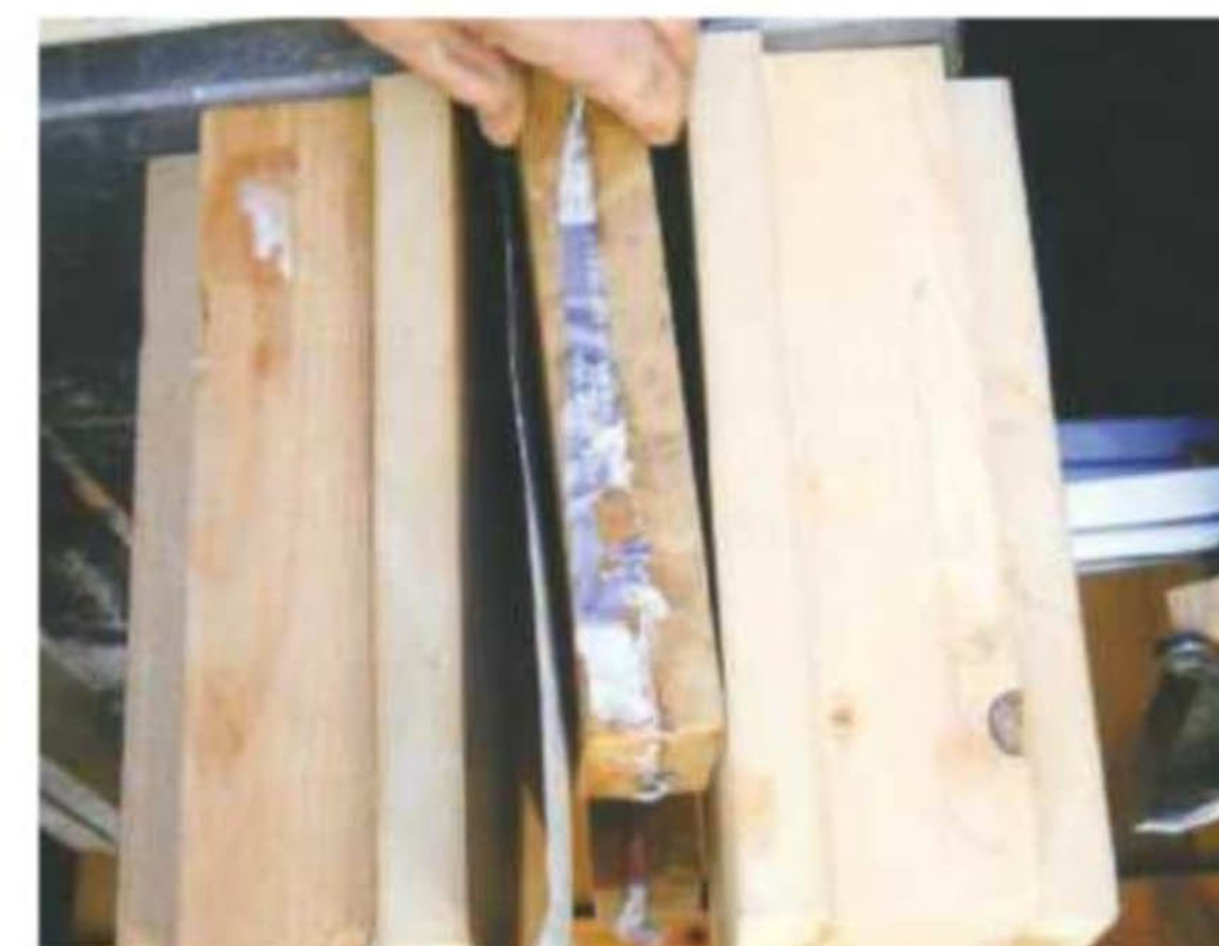
1 Place the oak in between the scrap wood; the paper makes the joints easier to split apart later
