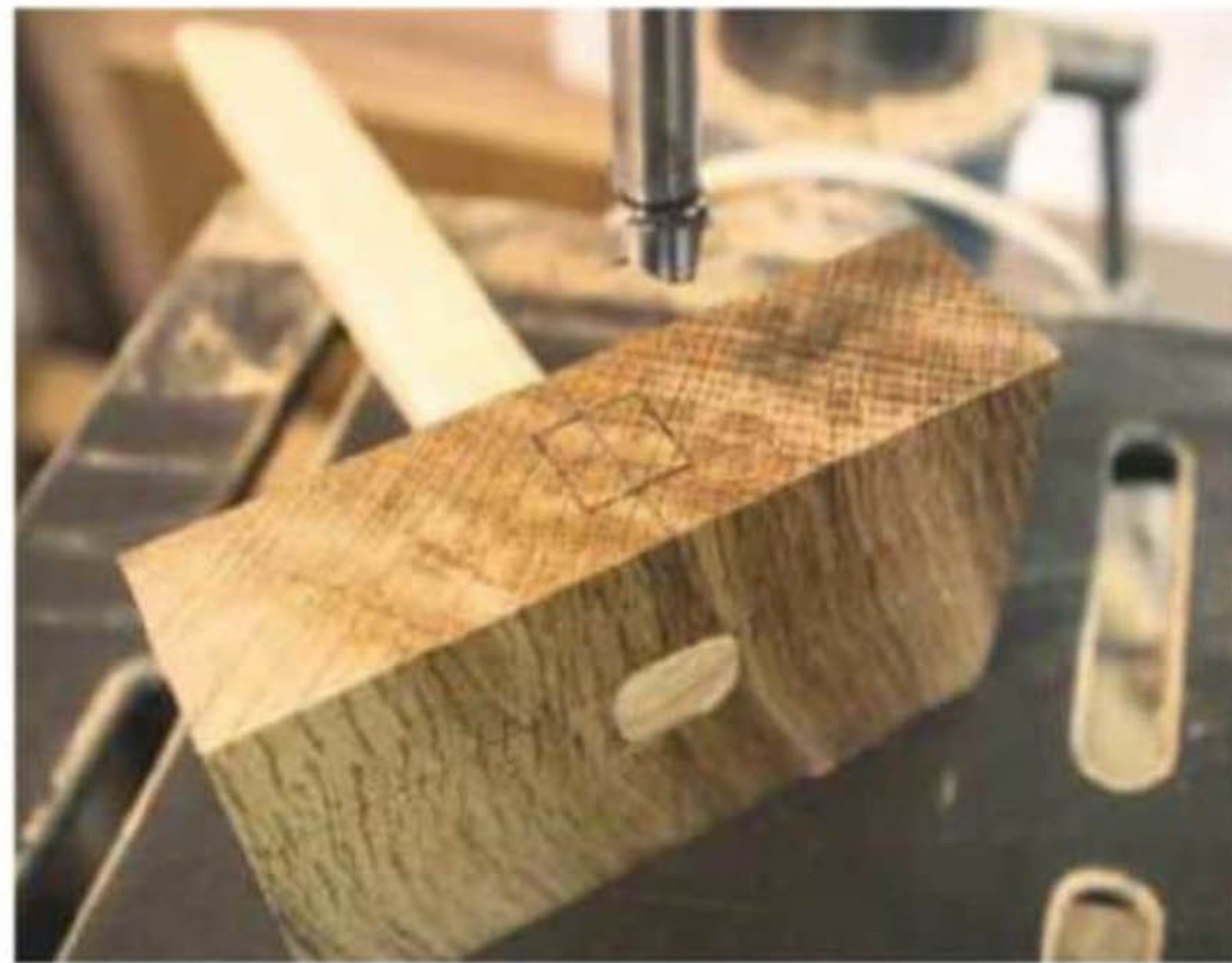
8 The top mortise ready for drilling with a 15mm Forstner bit
