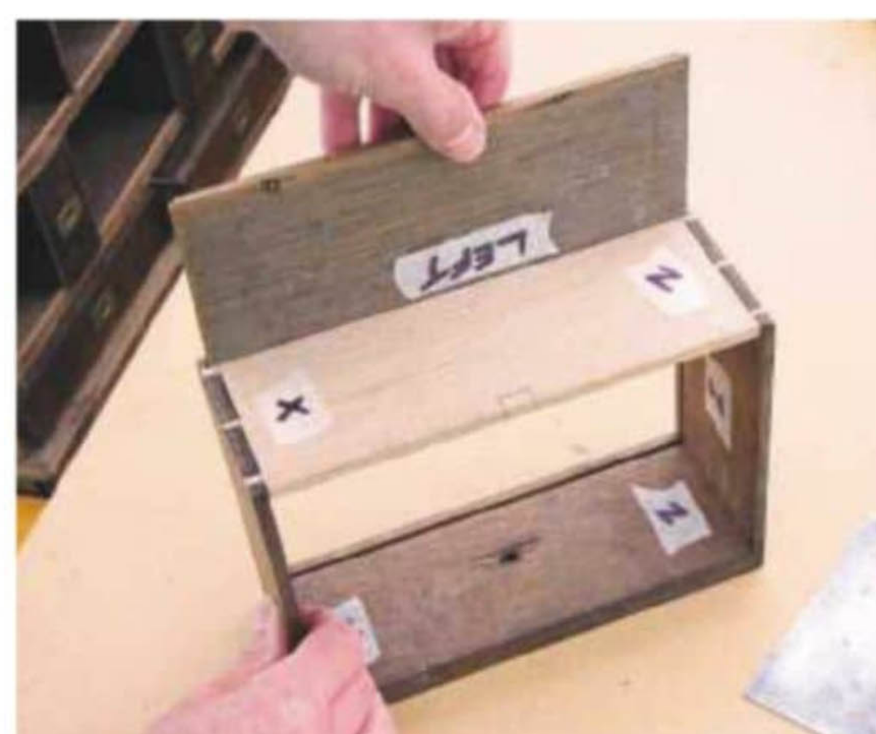
28 Slide drawer bottom into the grooves and check for square; avoid forcing parts together
