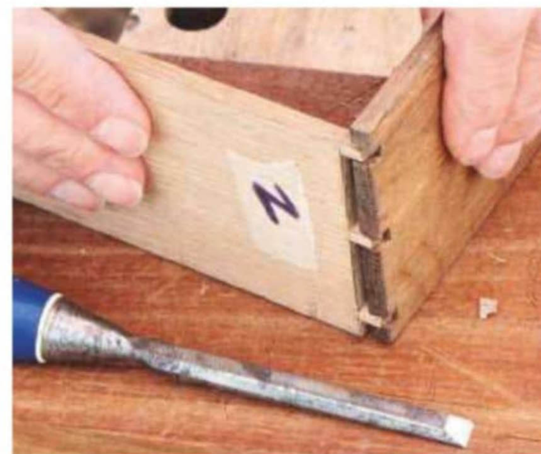
27 Check back and side pieces fit together snugly and pare joints, if necessary, with a chisel
