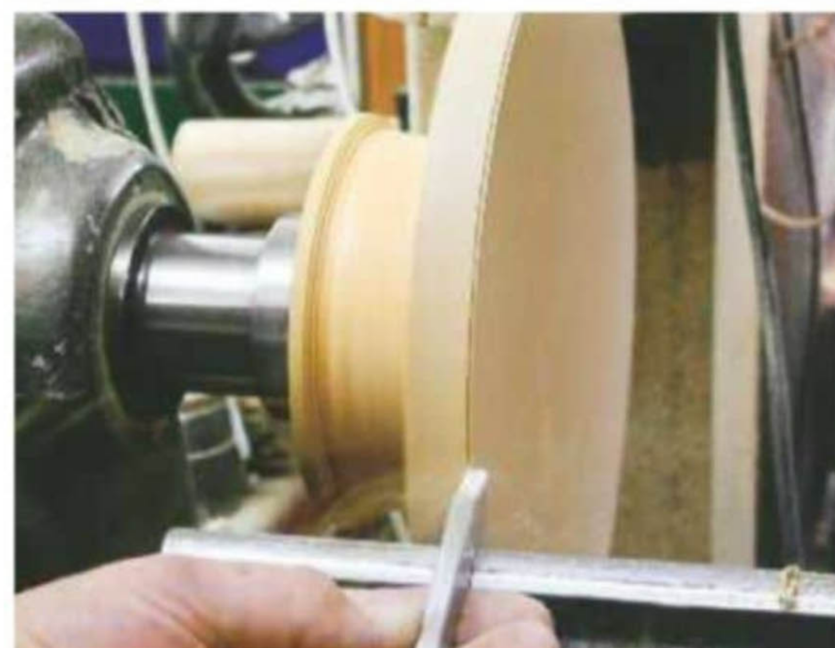
10 A parting tool will turn the two fillets...
