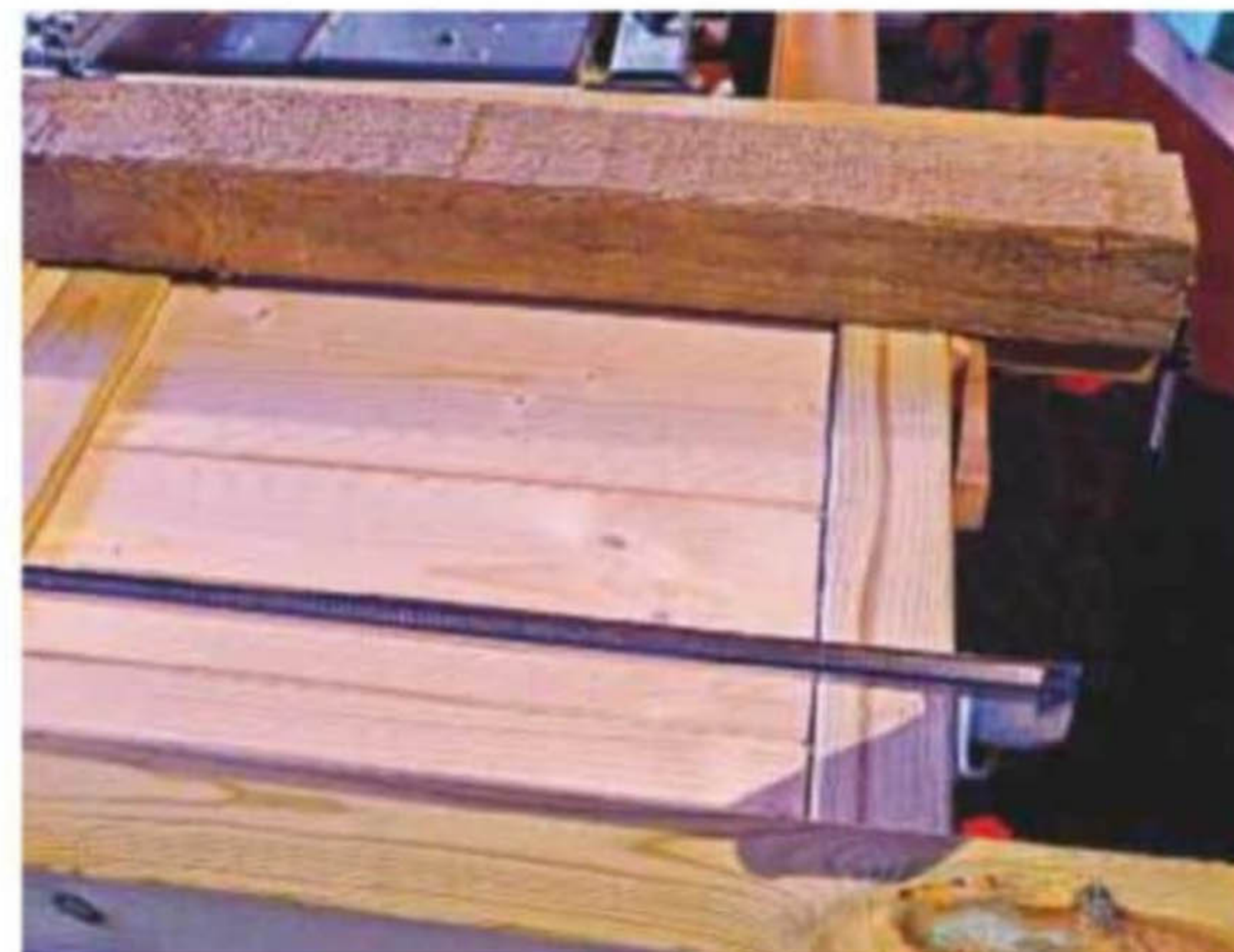
14 Makeshift clamp – I ran short of a clamp for the capping pieces, so cobbled together a Quick-Clamp using wedges to generate the pressure
