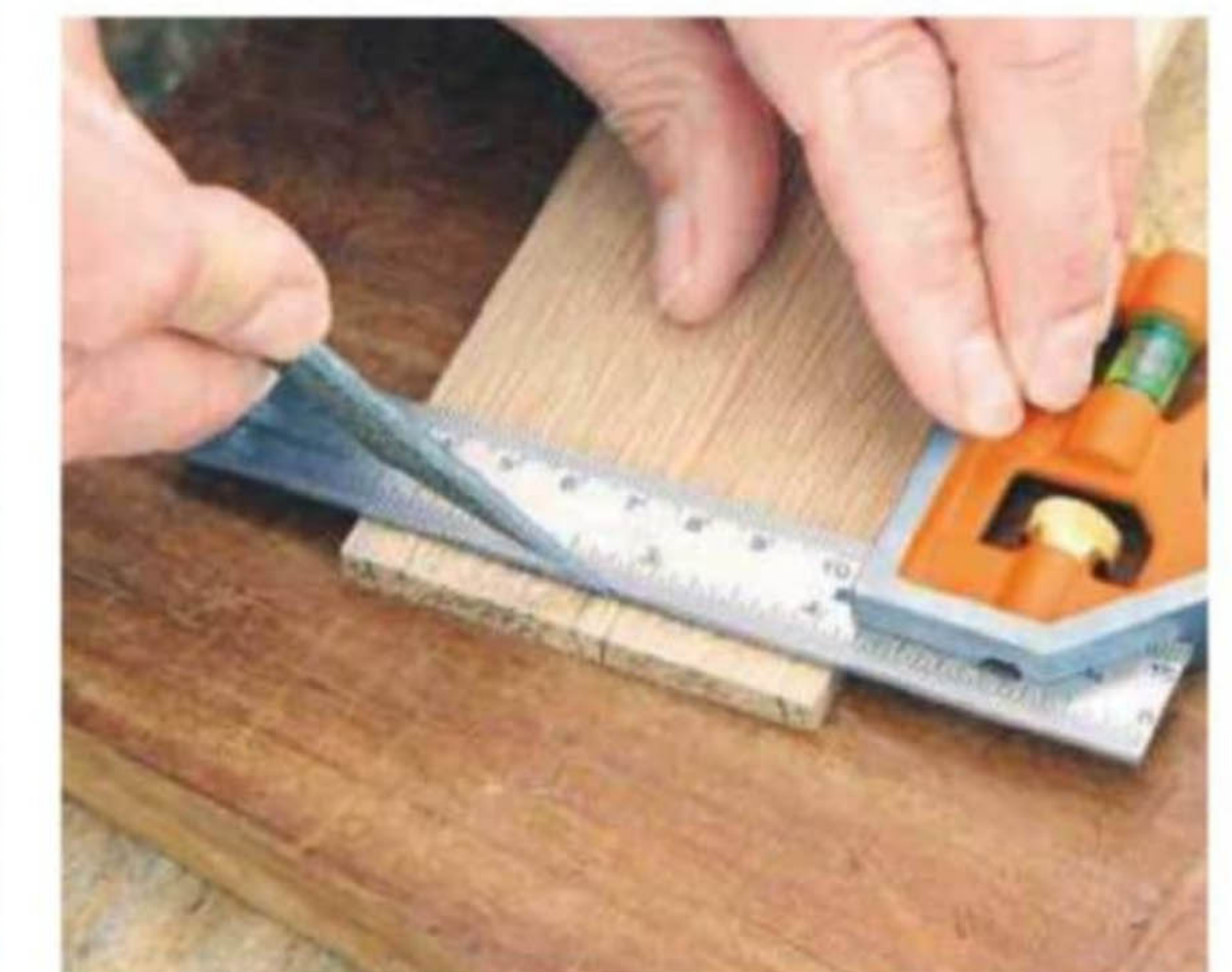
24 Scribing shoulder lines across the back piece with a marking knife helps give crisper joints
