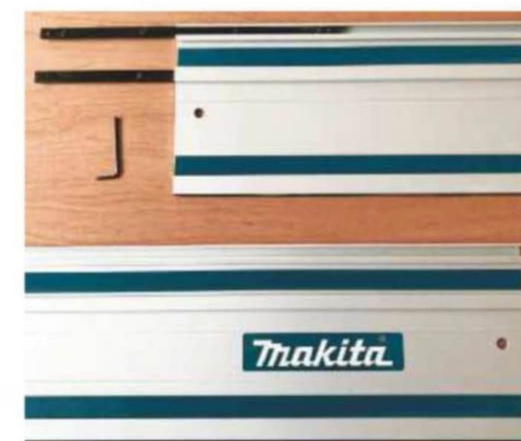
Both rails, connector bars positioned and Allen key for altering
