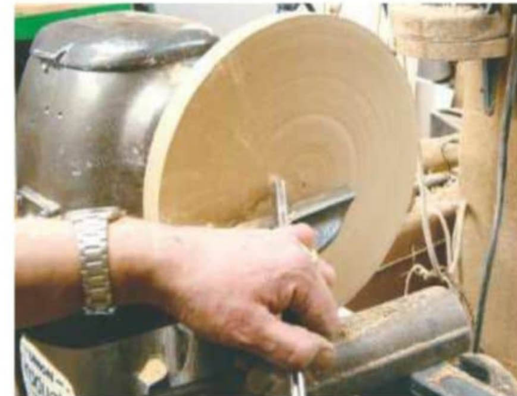
9 Mount the shelf onto a glue chuck and turn it so that it's absolutely flat
