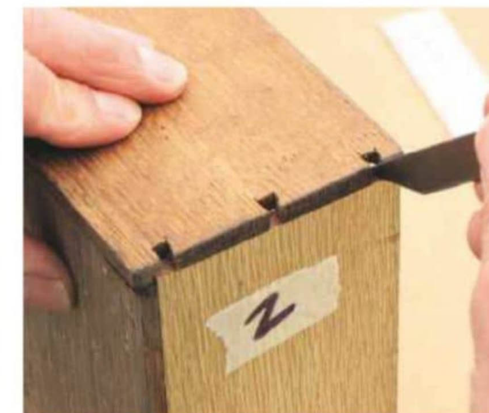
23 Loosely assemble the drawer and mark the position of pins on ends with a sharp marking knife
