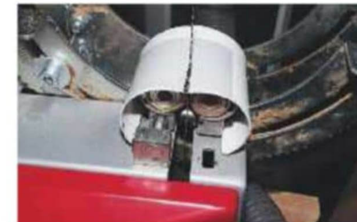
Cut out plastic tube fitted over lower bearing guide, which provides a shield from sawdust
