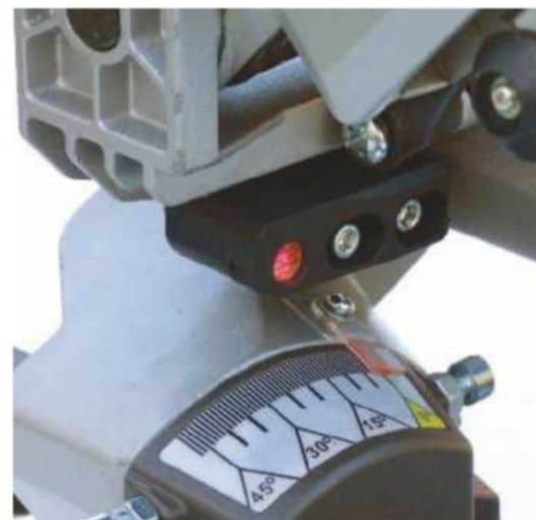
Calibrating the laser is slightly fiddly with three hex keys, only one of which is included
