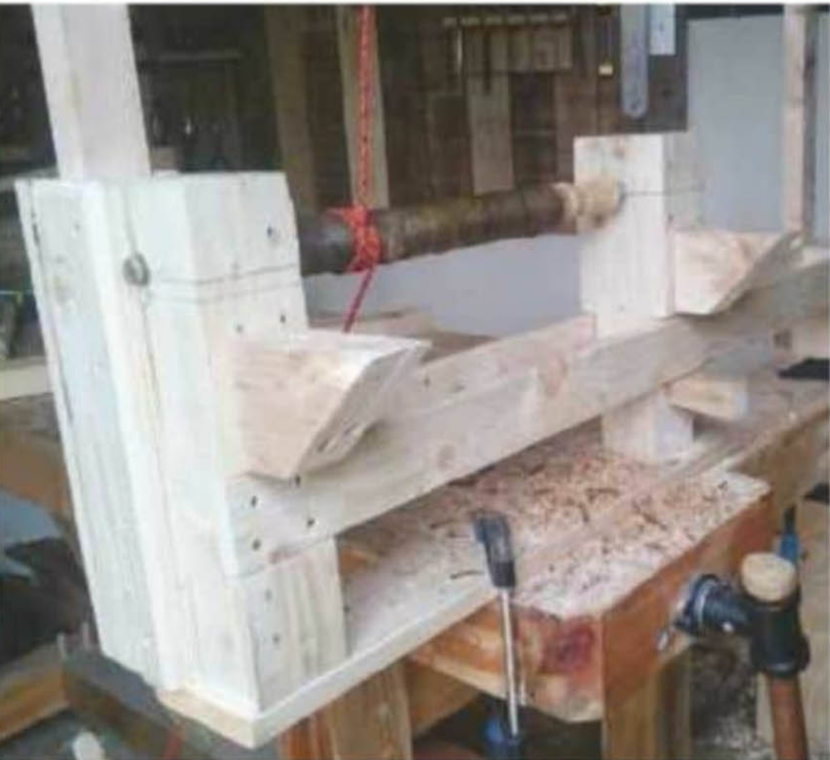
PEDAL POWER Clint Rose makes use of pallet wood to build his very own bench-top spring pole-lathe, which can handily be packed up and put in the back of a car
