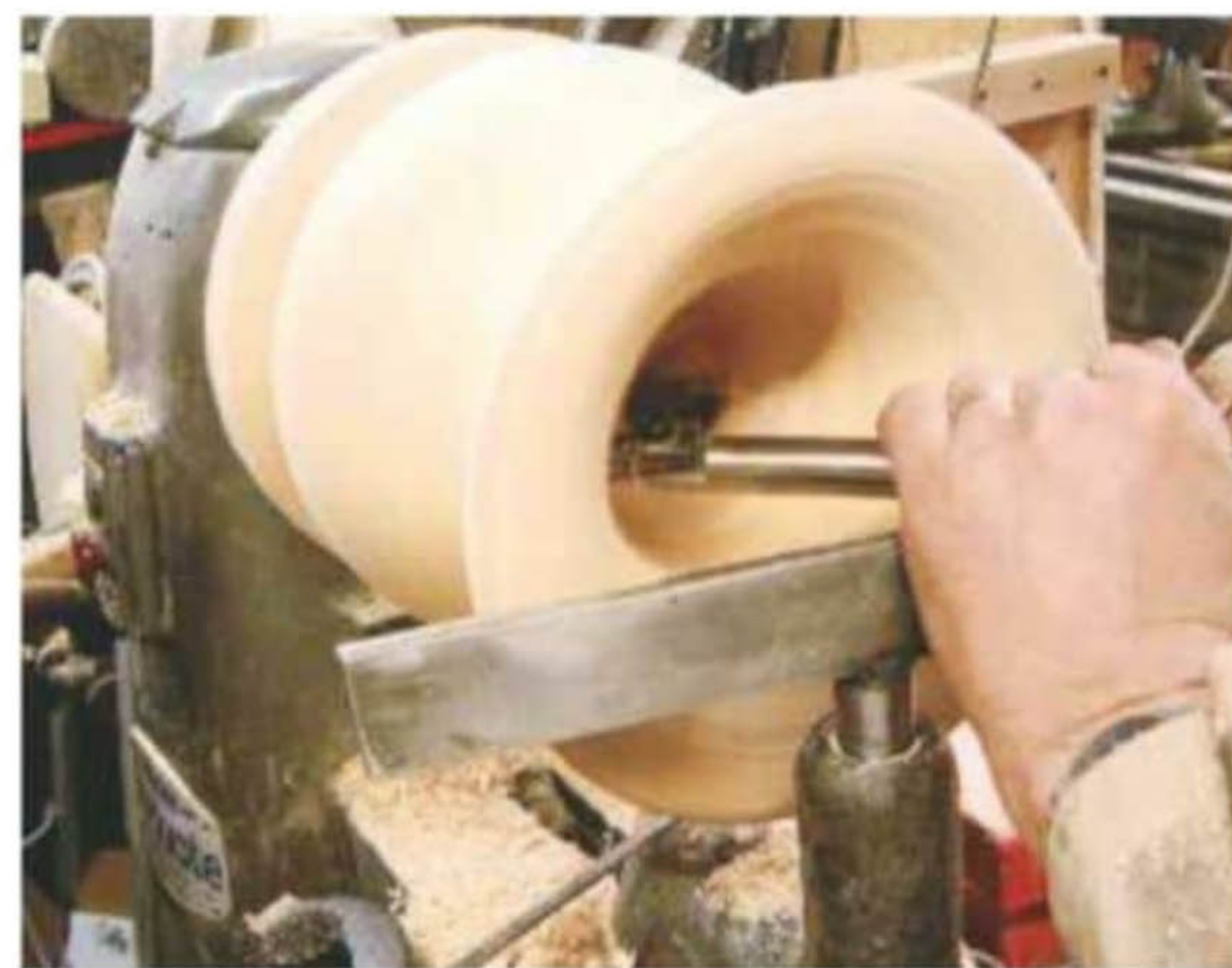
5 The quickest way to turn the inside of the block is with a hollowing tool
