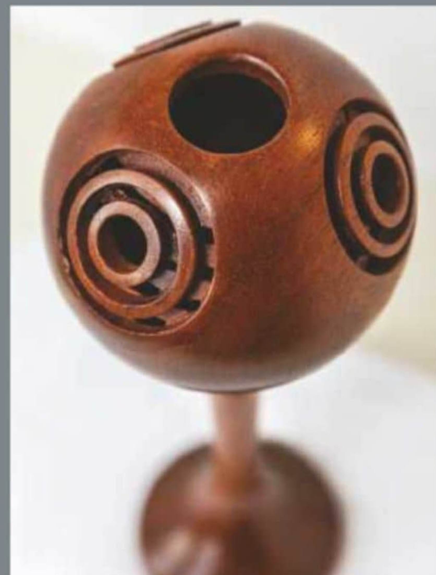
Edwin Barber's essay in mahogany was parted into two hemispheres, that were hollowed and inscribed with grooves, which – once the halves had been rejoined, and the whole remounted on the lathe – intersected with the circles turned on the outside of the sphere, creating a lattice
