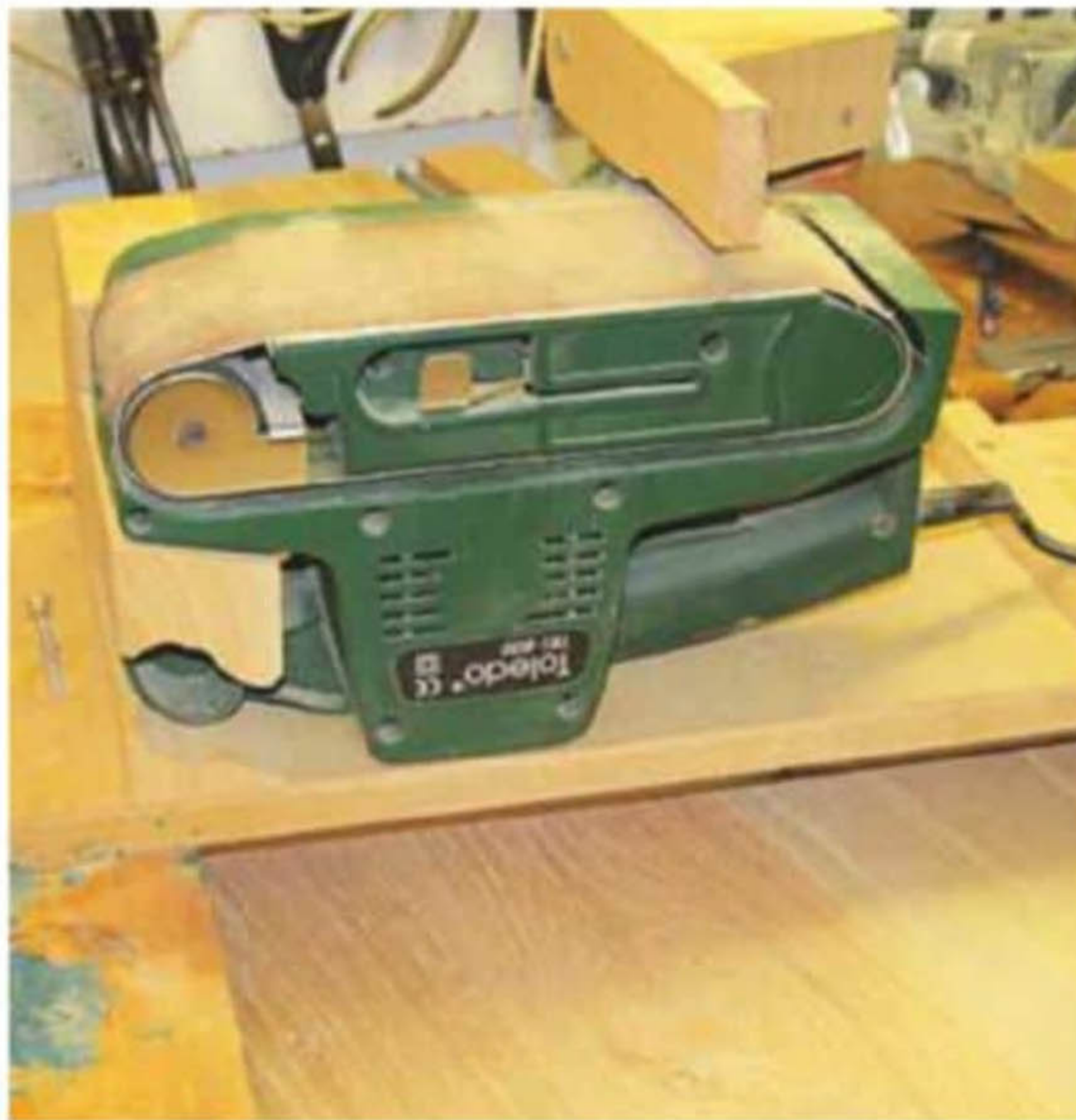
Michael's small electric belt sander mounted in a frame
