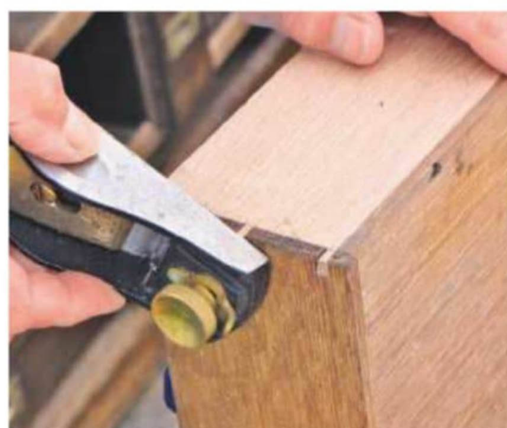
32 When glue has dried, trim joints with a block plane; check drawer slides in carcass opening
