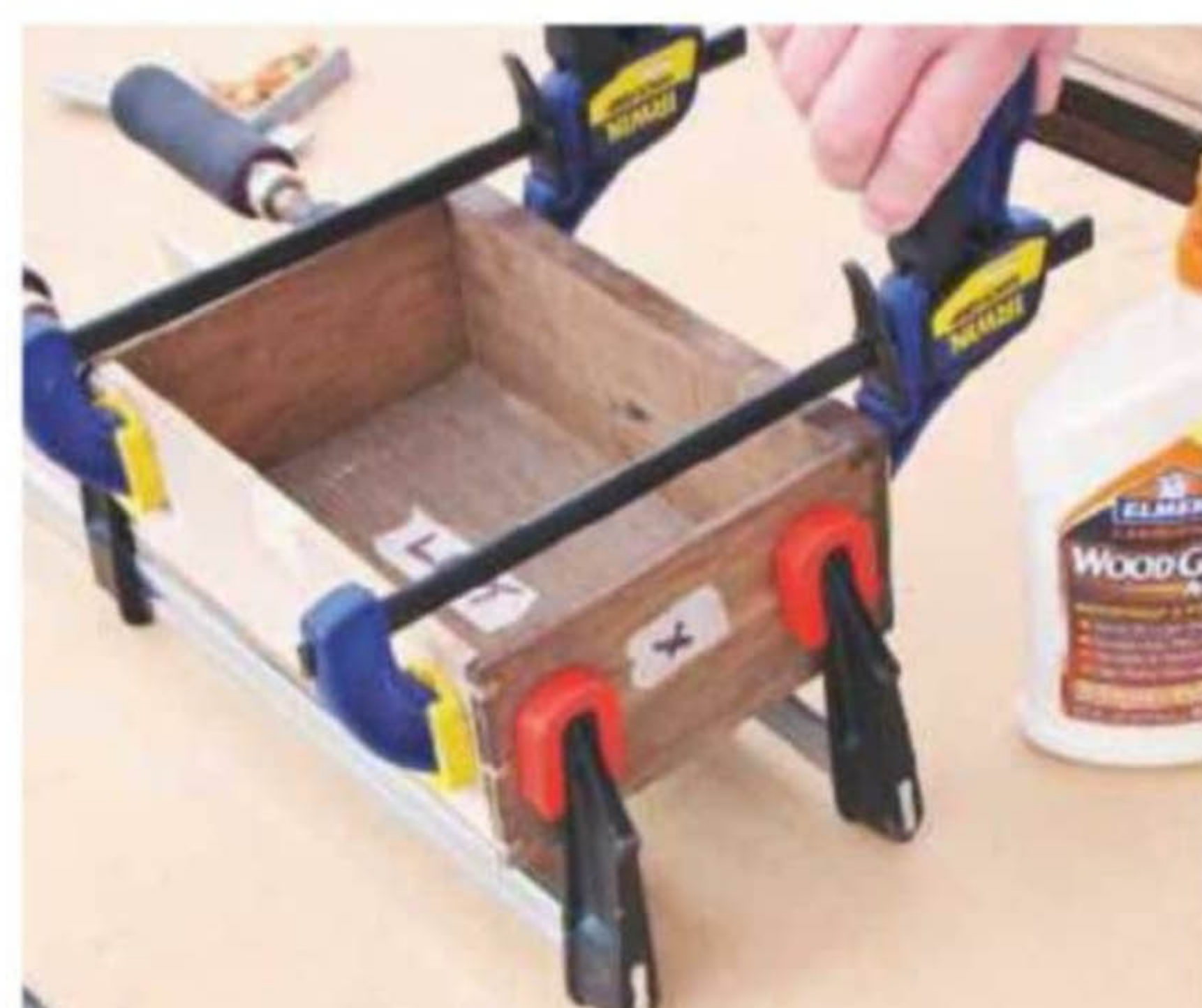
31 Cramp drawer together, across ends and front to back; check for square and adjust
