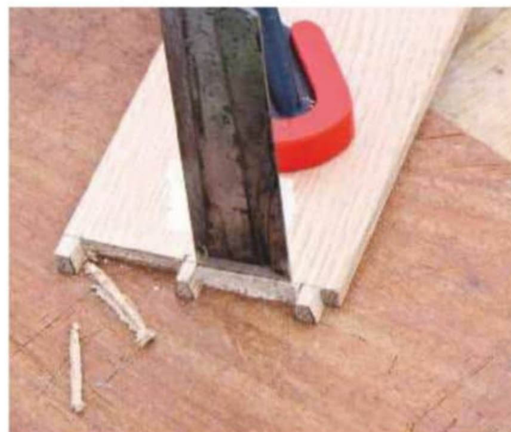
26 With a chisel vertical on the shoulder line, chop downwards; turn over oak to complete the cuts
