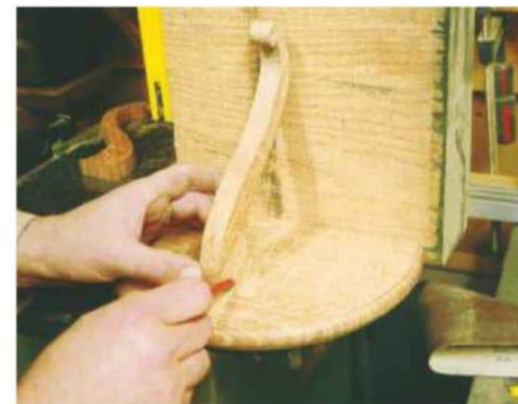
14 ... and then pencil around the bracket and mark the joint holes
