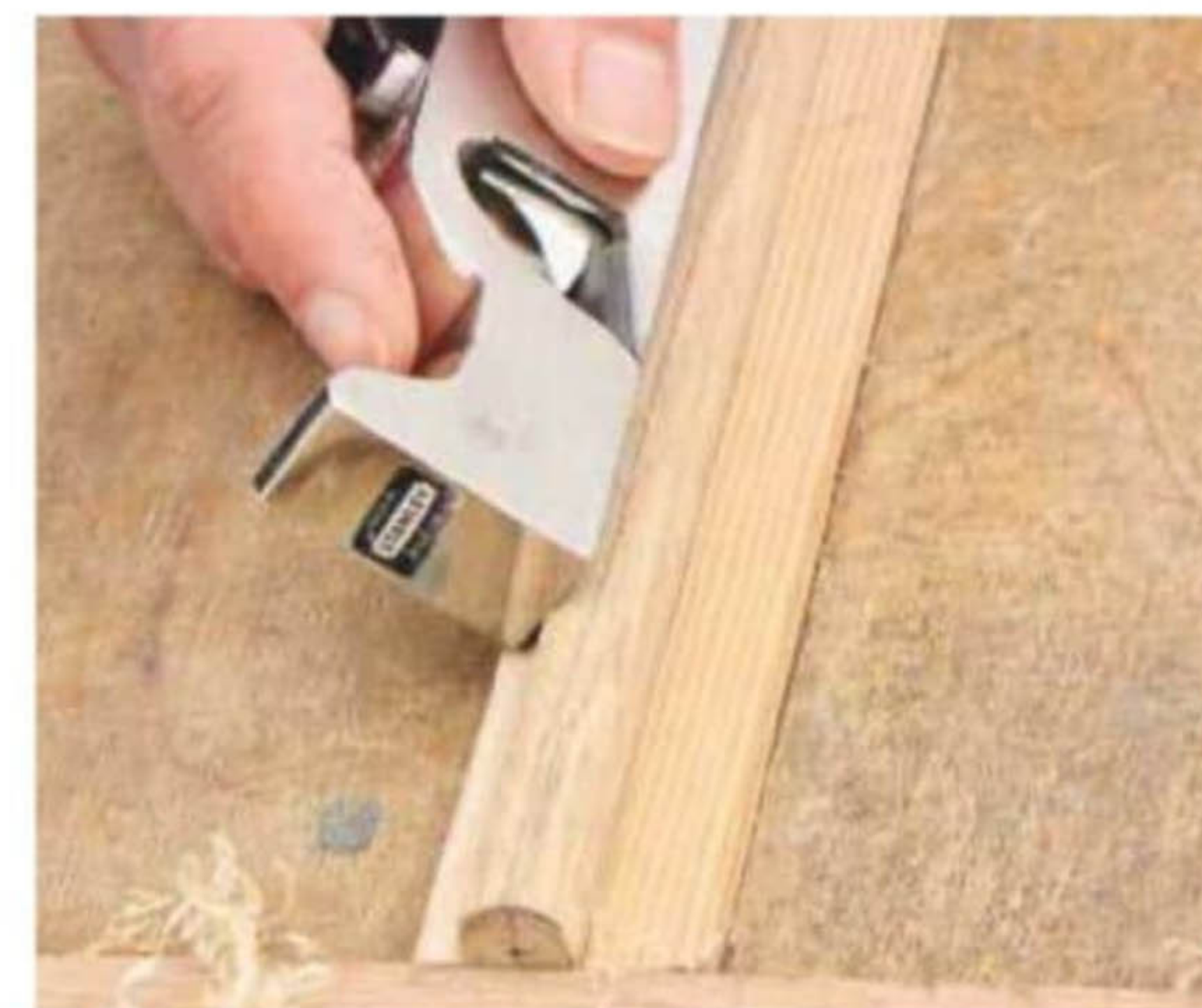
6 Use a combination of router table, shoulder plane and abrasives to match the exact profile
