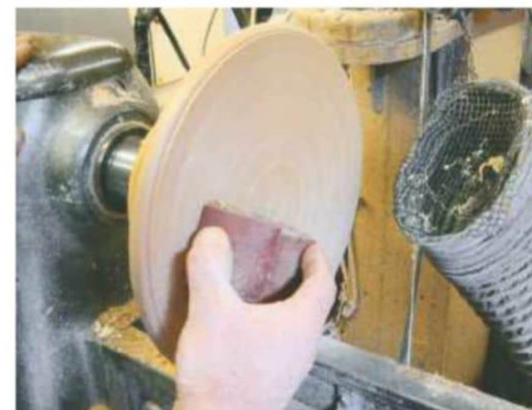
12 The quickest way to flatten the surface is to wrap abrasive around a cork block
