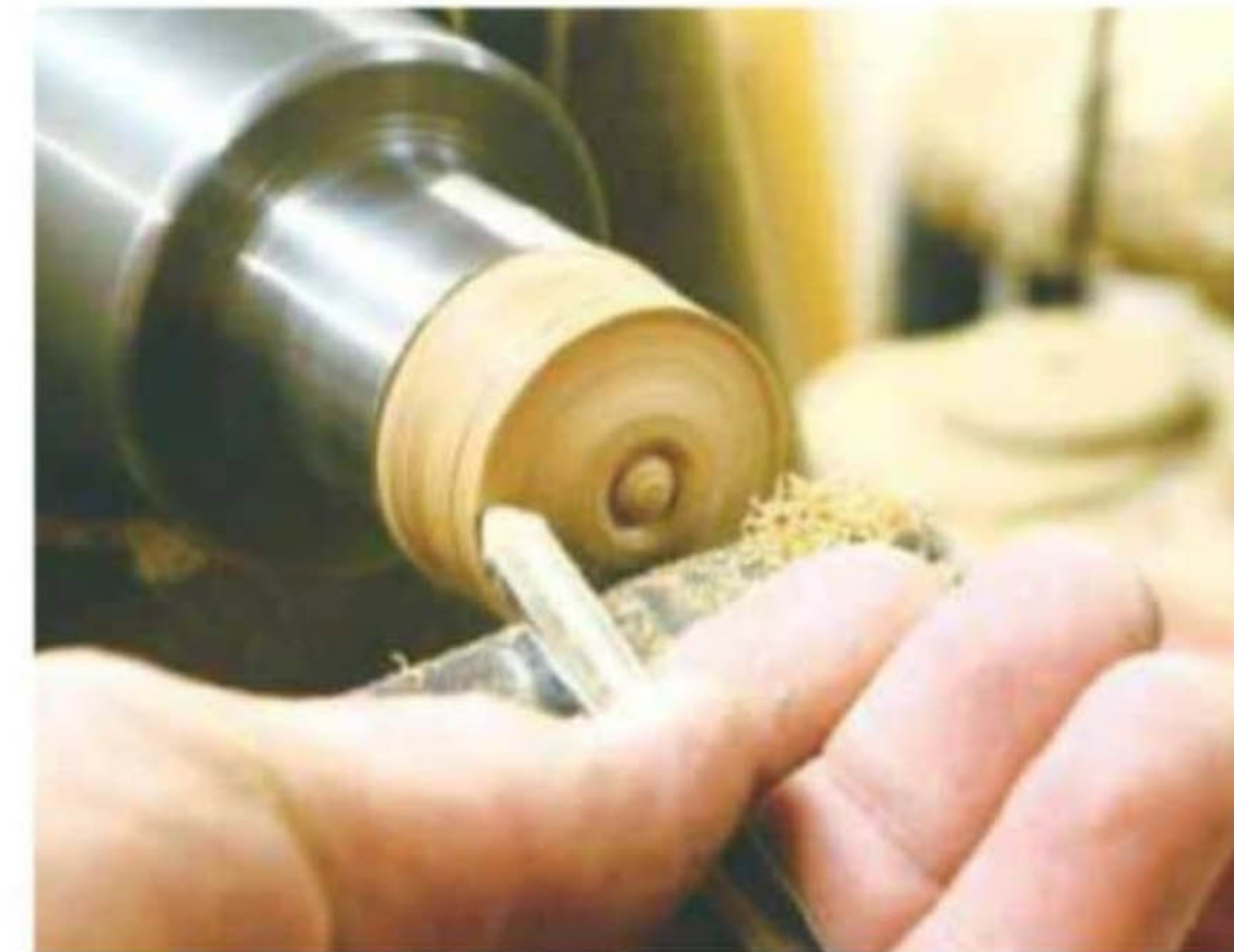
16 Hold the roundels on a screw chuck. These are delicate so take your time...
