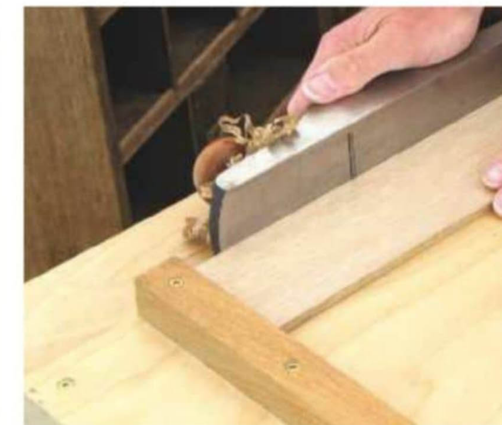
20 Thickness new oak for the back down to 6mm, then shoot face edge with a bench plane
