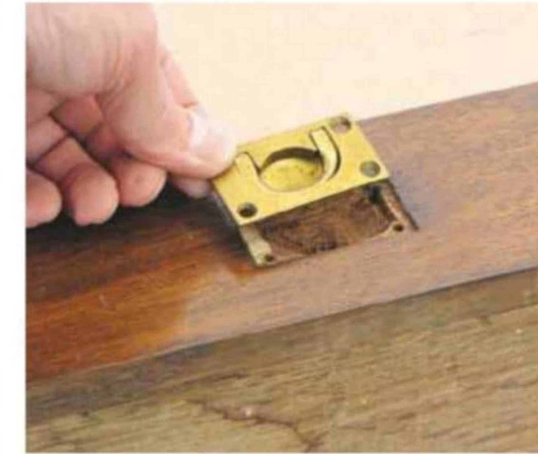
14 Carefully remove brass screws and lift off the handle; recesses had been crudely cut
