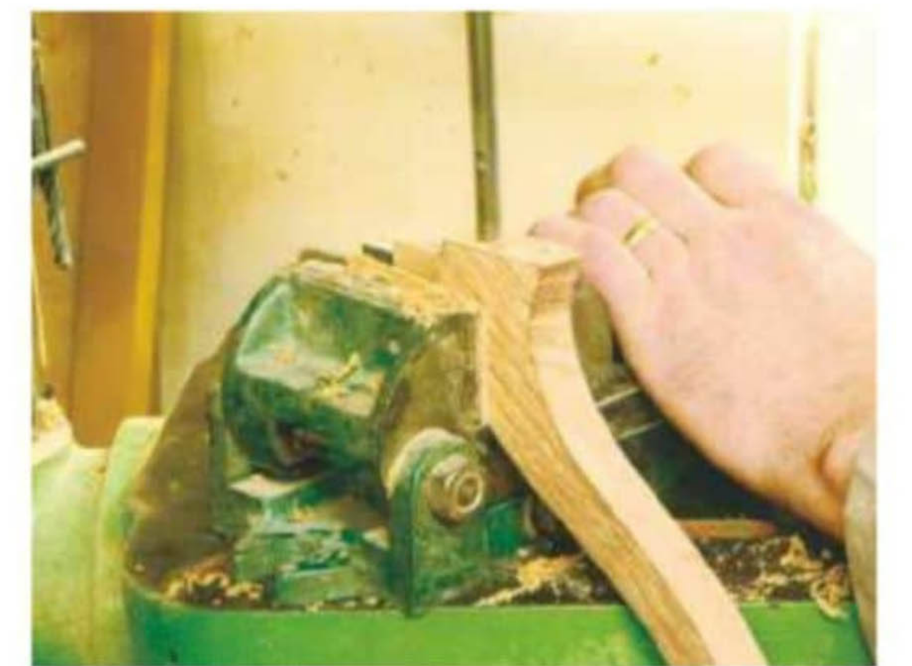
15 Hold the bracket firmly in a machine vice and drill two 10mm holes
