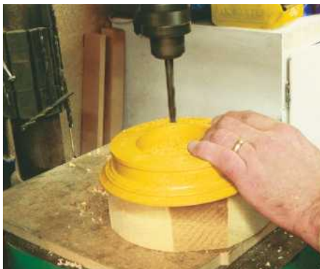
7 Set the depth stop on the pillar drill and drill the holes for the pillar spigots
