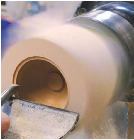
10 I need a little step for the lid to sit on and here I'm creating it with the 10mm skew chisel. I'm looking to get a perfect finish off the tool, so I make sure the tool is very sharp and that I take light cuts
