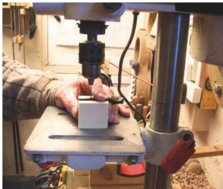
60 Each peg must have a 1.5mm hole drilled for the string
