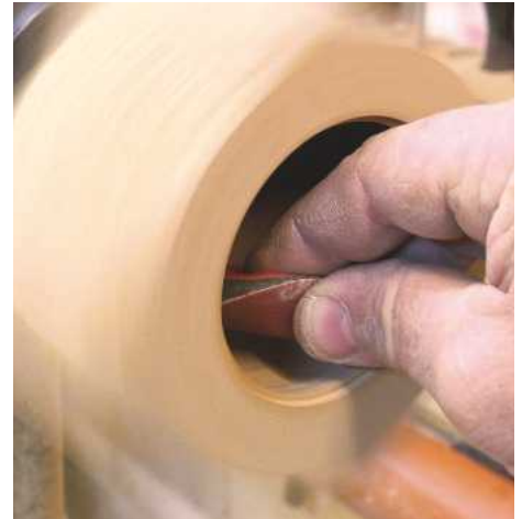
15 First, slow the lathe down and with the work stationary lightly hold the pad inside the piece. Start the lathe up and sand the inside surface, being careful not to touch the rim. To stop you trapping your fingers, keep the abrasive around the 8 o'clock position
