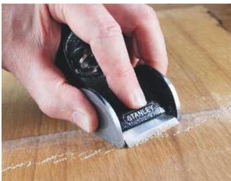
8 Chisel-planing glue from a reclaimed board
