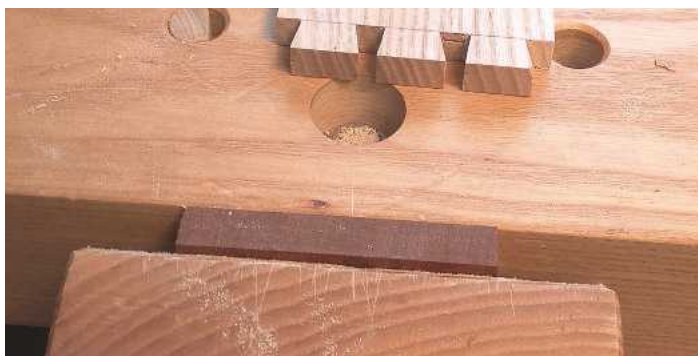
1 Set the tail piece in the vice level with the bench top
