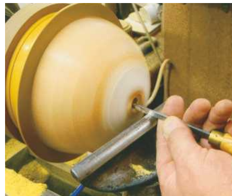
18 When you turn the hole for the finial, leave the masking tape in place for security
