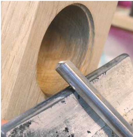
13 The 60° bevel on this 10mm bowl gouge solved both of these issues and meant that I could easily clean up the excess stock in the bottom of the bowl, even the very slowly revolving timber in the centre
