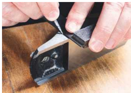
3 Scribing in line with the rear of the mouth
