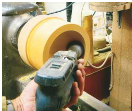
11 Power sand the inside. Work through different grades to ensure a good finish
