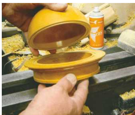
15 Put a little PVA glue on and clamp the two together before leaving them to set
