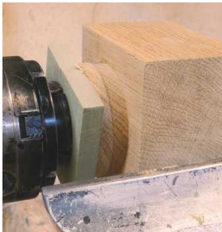
17 This needs to be a snug fit. You don't want it to be really tight, though, as it's cross-grain and likely to go slightly oval after it's been turned, even if the timber is very dry
