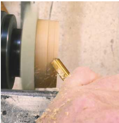
16 Once you are happy, mount the lid onto a screw chuck. Here I've used a MDF spacer to shorten the screw. Make the piece round and turn a shoulder down to match the hole in the box
