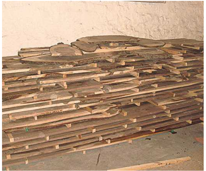
Stickering wood in a basement
