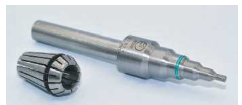
There are accessories for this lathe and in this article I am using a friction drive with the appropriate collet
