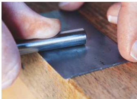
33 Drawing the edge with a burnisher
