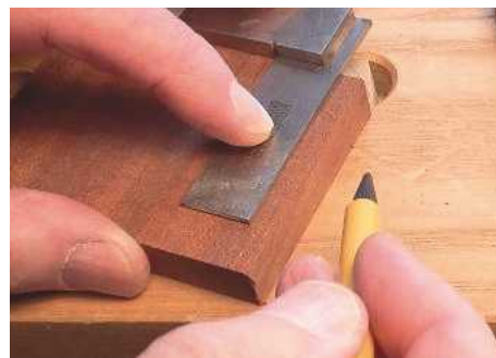
4 Run some guide lines for the saw down to the shoulder using a pencil and square
