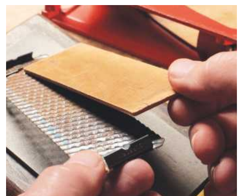
24 A plywood pressure plate covers the blade
