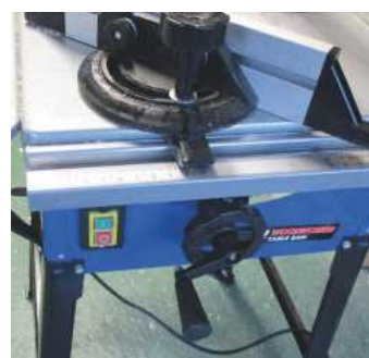
The stop switch is not well placed
