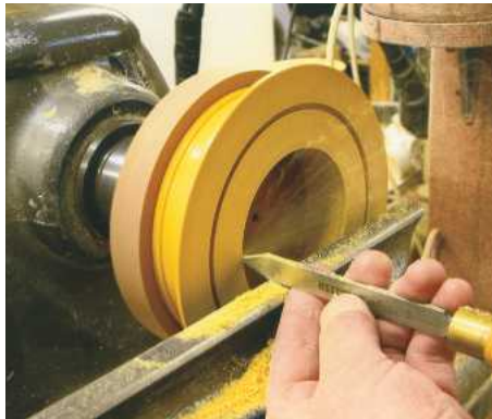
5 Remove the rest of the architrave's centre with the parting tool
