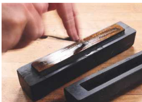
16 Sharpening on a restored whetstone
