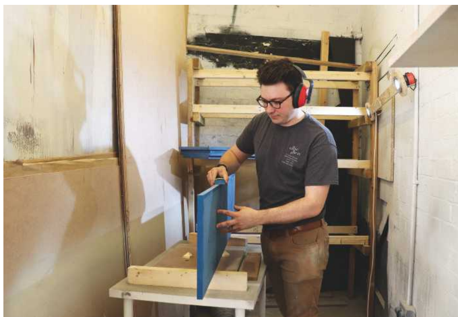
Ollie preparing and sanding blue Valchromat boards ready for a clear lacquer coat
