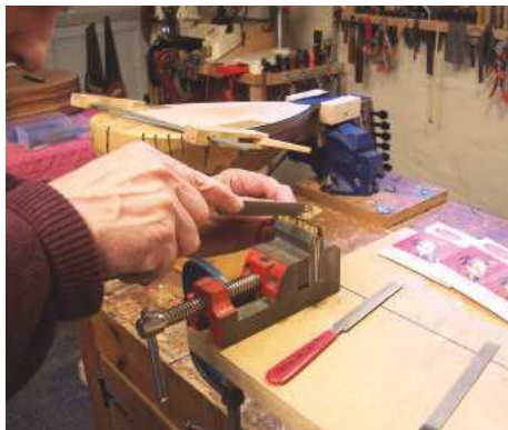
59 Filing the string slots in the top nut
