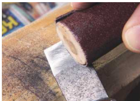
14 Removing rough marks from the grinder
