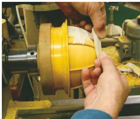
17 Glue the ribs onto the half-sphere and hold them in place with masking tape
