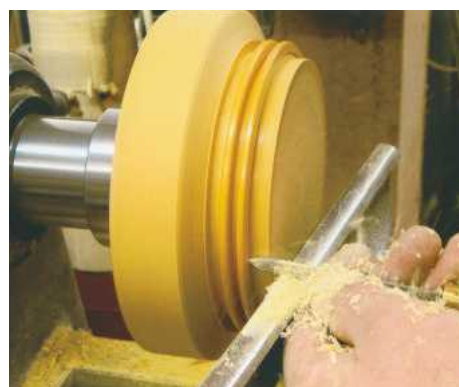
16 Fix a piece of pau amarillo to a screw chuck and turn the ribs using a parting tool
