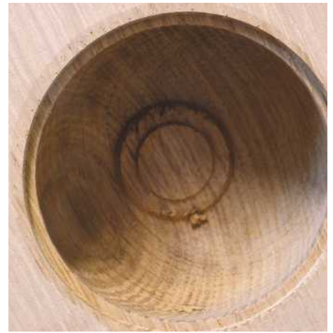
12 I struggled to get to the bottom with the 6mm gouge because the overhang caused the tool to chatter. Also, the 40° angle on this tool makes it difficult to get the bevel in contact with the wood
