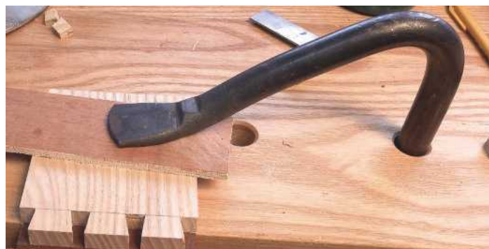
2 Position the tail piece over the end of the pin piece – I prefer to secure it with a holdfast
