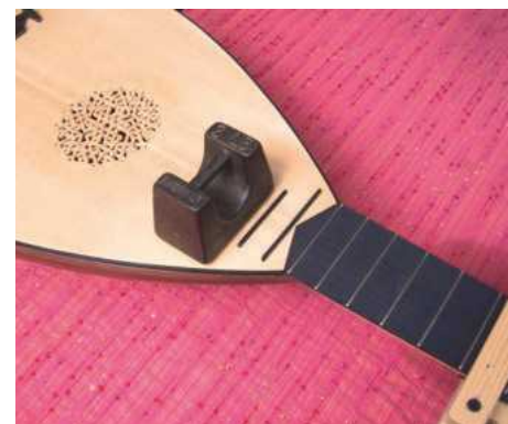
52 An old grocers' weight is useful to hold the frets in place as the glue cures
