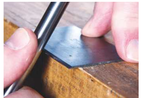
34 Turning the new hook
