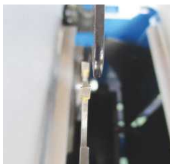
Unclear instructions resulted in a misaligned riving knife
