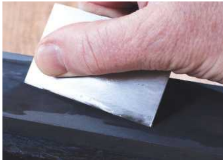
31 Whetting the bevel on the oil stone
