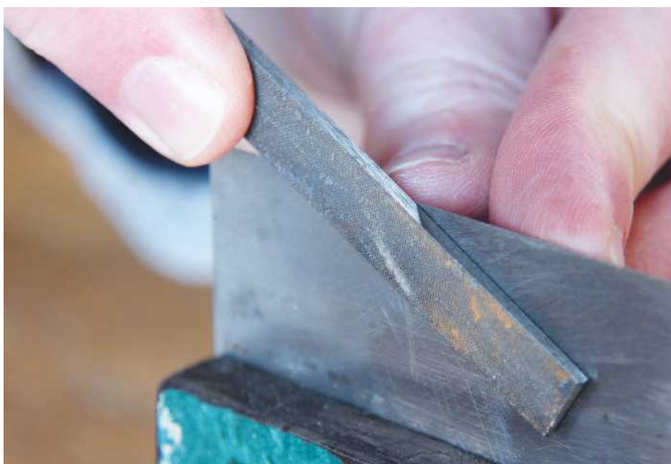
29 Filing down remains of the old hook
