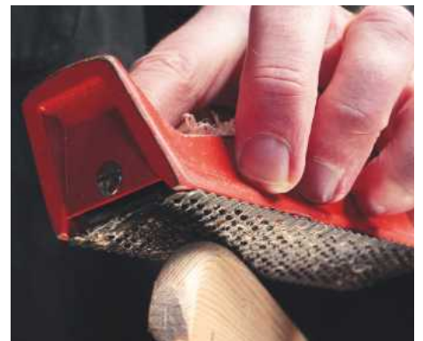
23 The Surform 111A is a handy rounding tool
