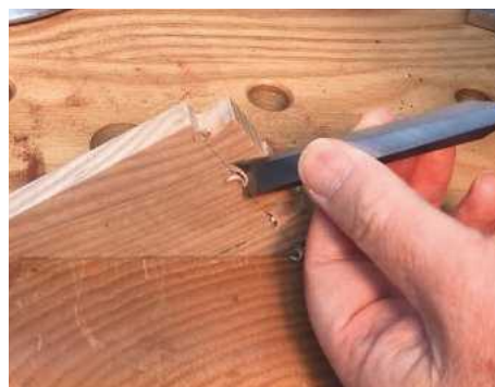
12 Starting just behind the end of each tail, cut a small, tapered chamfer back to the shoulder...
