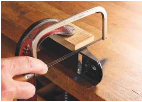
4 Guiding the hacksaw with a wooden block
