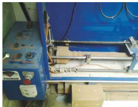
Pro-Am lathe to create long posts
