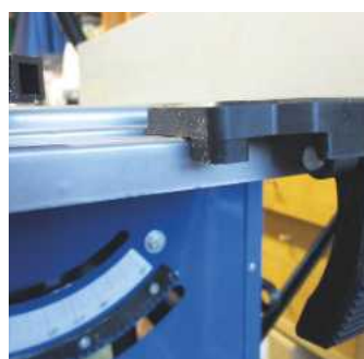
The fence lever needs a firm push to lock it in place
