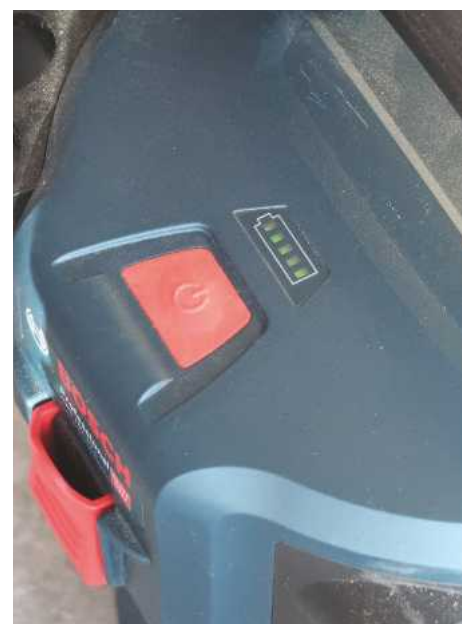
The power indicator on top of the vacuum shows the battery level remaining
