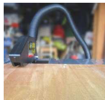
The extraction hose gets in the way of wide boards
