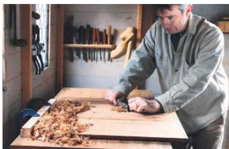
28 Stripping the finish from a reclaimed oak board
