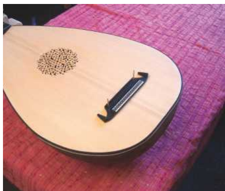
57 The bridge held in place by two cocktail sticks that are later snapped off
