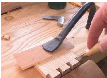
3 The flat side of the marking knife held against the tail allows very precise scribing
