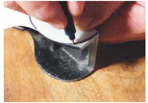
6 Marking the second side using a template
