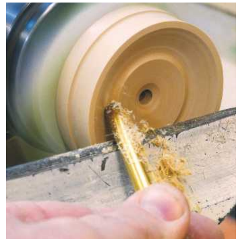
18 To lighten the lid, hollow out the underneath with the small bowl gouge; this will expose the screw chuck hole but that can be dealt with later. Now's your last chance to sand and finish this part
