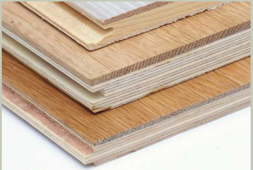
The top layer (lamella) of engineered hardwood is usually oak, walnut or maple, which can be from 2 to 5mm thick
