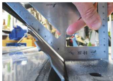
At full tilt the blade does not quite reach 45°
