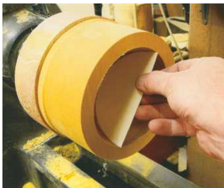
10 ... use your template to check the shape of the inside of the dome
