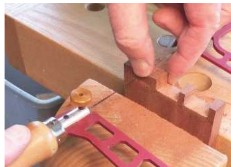
6 As with the tails, the fret saw removes the bulk of the waste. Use thumb pressure against the chip to break it away before the saw blade reaches the pin
