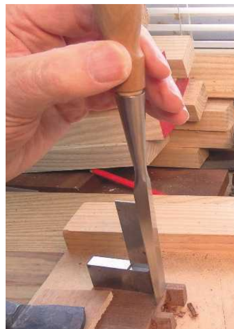
10 For the final cut, position the square behind the chisel and sight through – aim to under-cut very slightly to create a tiny hollow on the shoulder...
