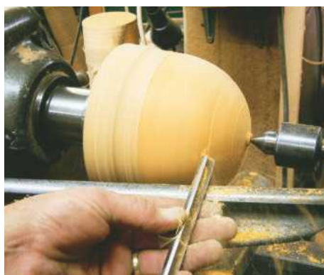
13 Reverse the half-sphere into a jam chuck and turn the outside. Once again...
