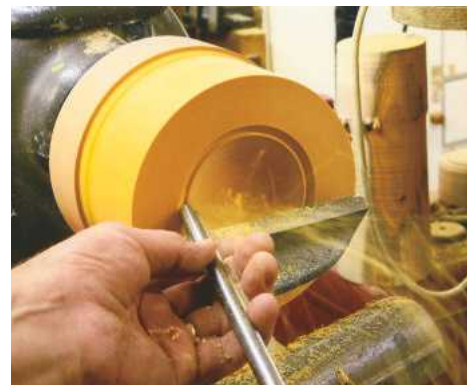
9 ... remove the centre with a 9mm gouge. Take slower cuts when nearly completed and...
