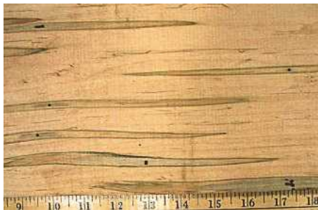
Ambrosia beetle staining in wood
