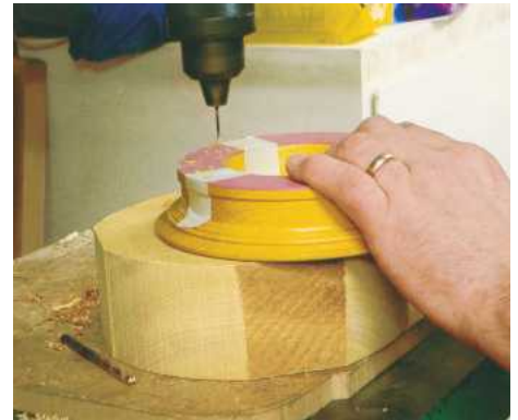
6 Use masking tape to secure the template while you drill the pilot holes
