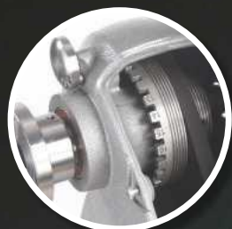
Heavy-duty spindle lock and 24 point indexing
