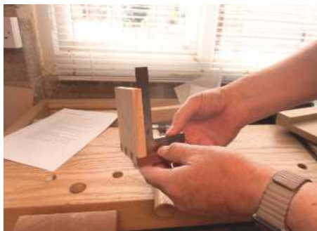
15 Finally check that the joint is square
