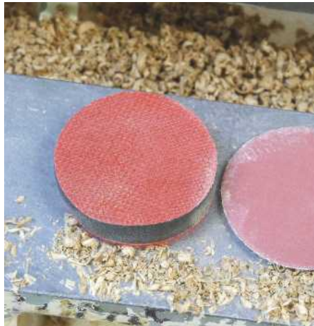
14 I'd usually power sand the inside of a bowl but the narrow entrance to this piece makes that impossible. I have many sanding devices and tricks and mounting an abrasive disc on a Simon Hope soft interface pad will do the job here
