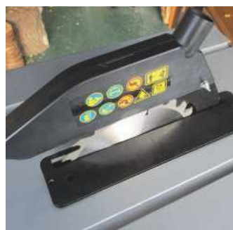
The crown guard in place
