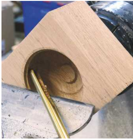
11 Undercutting the entrance to the box will make the inside look much better. This isn't an easy cut with a gouge but one worth practising as the finish achieved using it is much better than with a scraper
