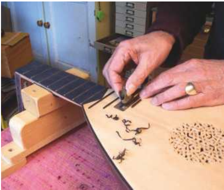
53 The ebony frets are brought to the same height as the nickel silver ones
