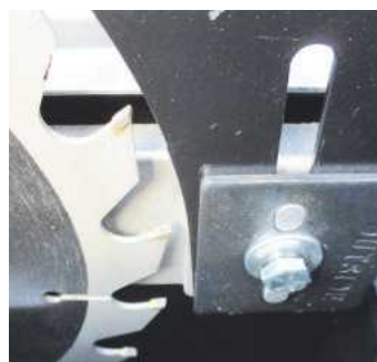
The clamp plate needs to be on the outside!
