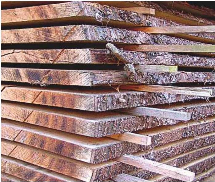
Drying through and through – cut boards on stickers
