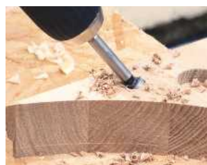
For angled holes you may need to drill a pilot hole first, though this shouldn't be necessary if using a pillar drill
