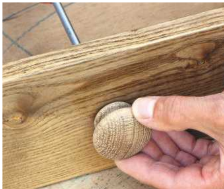
13 If some drawers are lighter than others, darken with coloured wax; screw new knobs to fronts to complete
