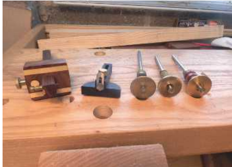
8 A range of cutting gauges at a variety of prices. The Silverline (left) is quite adequate at about £20
