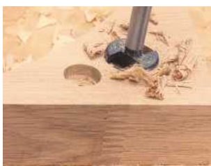
Unlike most drill bits they're guided through the timber by their rims, rather than a centre screw
