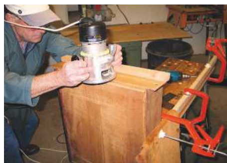
2 Using the router and jig to chop off the damaged section
