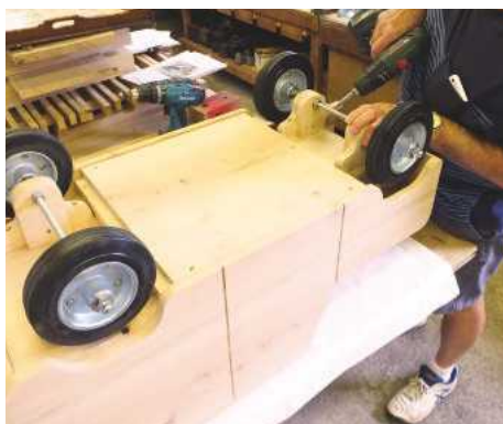
18 After some adjustment the axle assemblies are fixed onto the bottom
