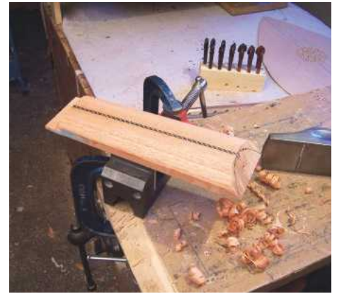
20 The neck inlay in place
