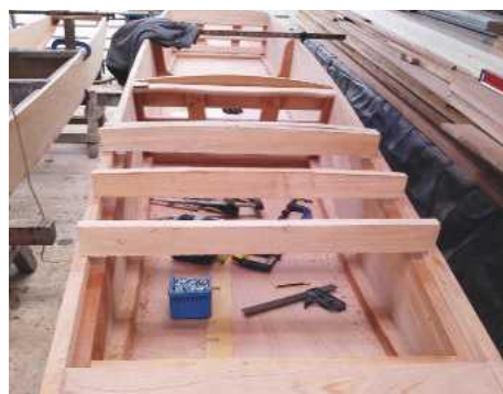
9 Initial marking out of the deck beams, before cutting the dovetails
