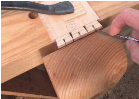
19 This Swann Morton No.4 handle and its long No.26 blade will reach where others won't go
