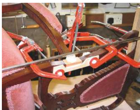
40 Gluing in the strengthening pieces
