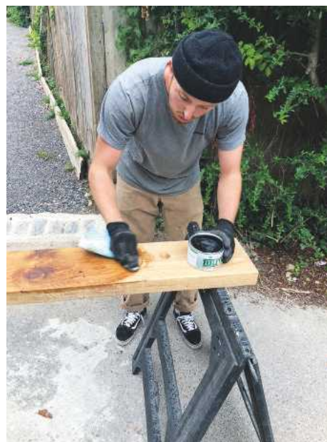
6 Waxing the 8x2 sanded joists (bed sides)
