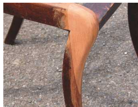
30 The new knuckle before finishing
