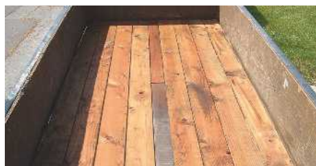
Engine oil was used to treat the floor of this trailer – a cheap and effective method
