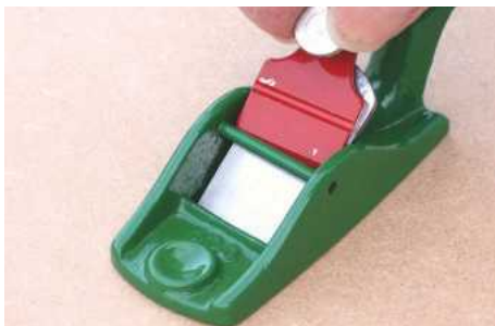
The blade is secured to the body by a cap iron that's tightened with a small thumbscrew
