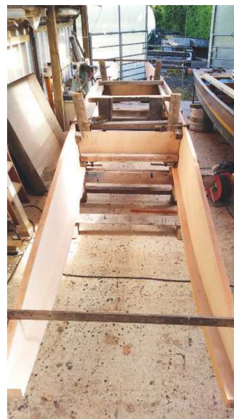
3 Sides set up in the jig with a sash cramp pulling the ends together
