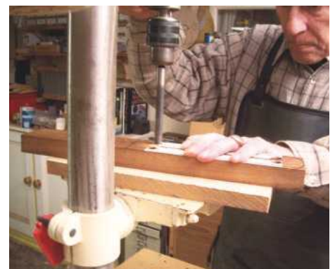
24 Drilling out the string slots...
