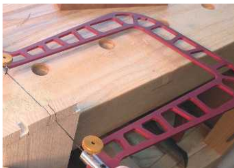
12 You'll need to remove the bulk of the waste with a fretsaw (not a coping saw). This Knew Concepts one is great but expensive...
