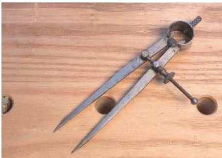
10 A good pair of dividers – another tool with a multitude of uses. Note the adjusting nut to prevent the setting slipping
