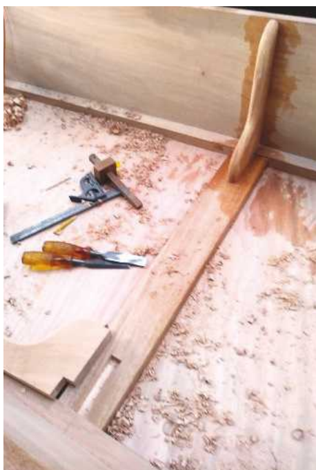
7 Knees are set into the housing of the central tread
