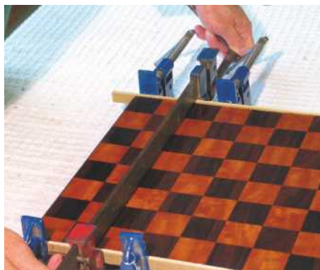
14 The loose edge pieces are glued back on
