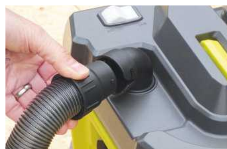
It's easy enough to swap from extraction to blower mode. You fit the floor nozzle, slide it over a grille and disconnect the other end of the hose
