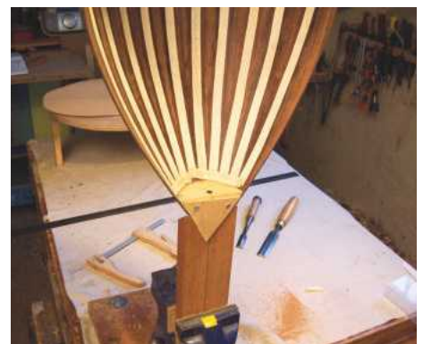
17 A small ply block prevents the neck join from sliding as the glue cures
