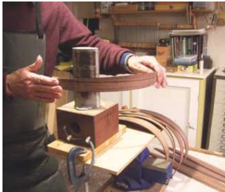
10 The ribs are bent on a hot iron
