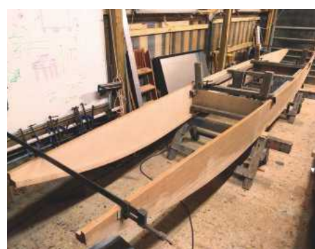
2 The sides are fitted around the jig before the ends are pulled to 610mm ready for fitting the huff
