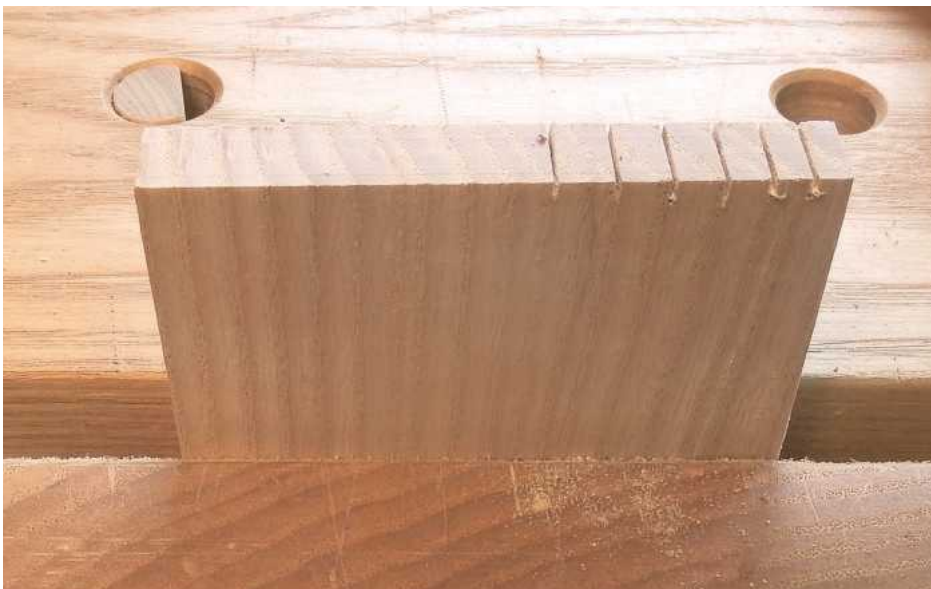
21 Practise on scrap until every cut is square to the face across the edge
