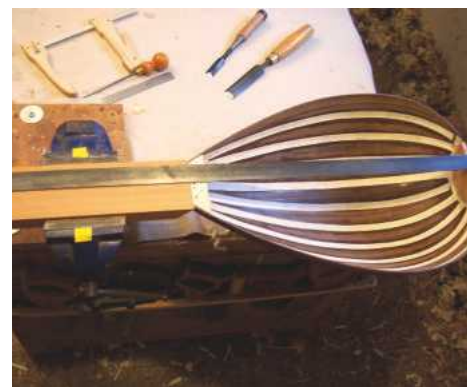
14 Linen tapes strengthen the joins
