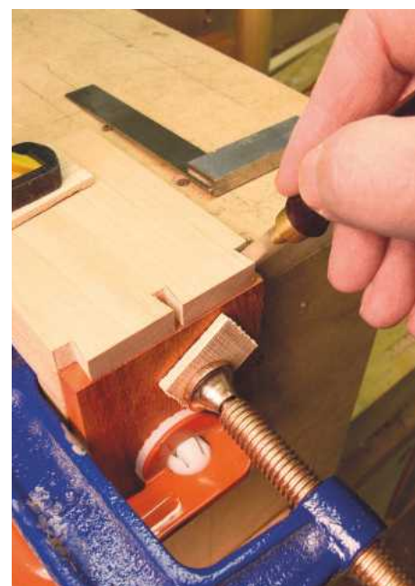
15 Some kind of marking knife is essential for scribing the profile of the tails onto the pin board
