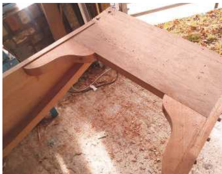
4 Knees fitted to the forward deck to strengthen the join and improve the rigidity of the punt
