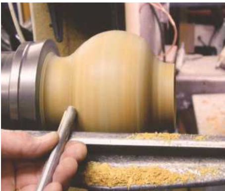
4 Shape up the outside with a 9mm gouge
