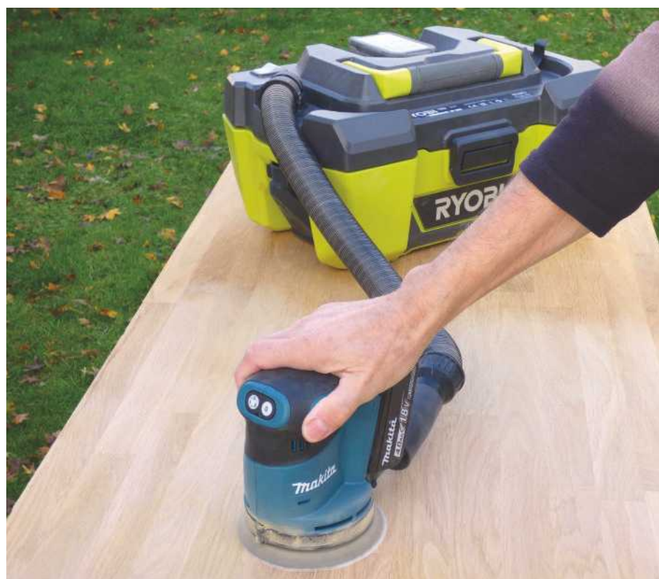
Hooked up to a random orbit sander it was just as effective, especially as you can position the extractor close to where you're working
