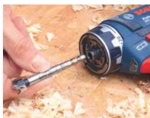
With the popularity of 1/2in hex-shank cordless drill/drivers, many bits will fit directly into an adaptor in the chuck
