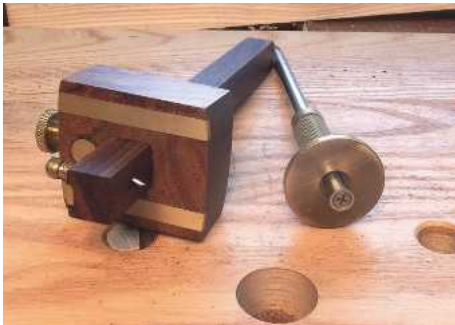
7 Make sure it's a cutting gauge, with a blade (left) or a cutting wheel (right) – not a marking gauge, with a pin
