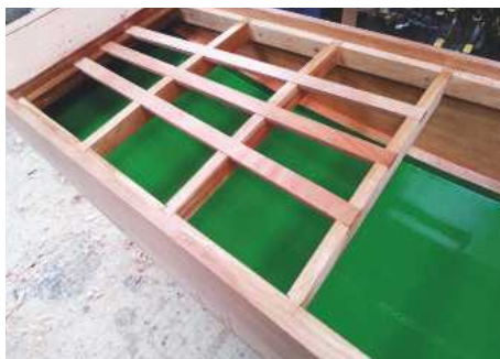
10 Deck beams in place and area underneath painted ready for the deck to be fitted. The underside of the deck boards are also varnished before fitting
