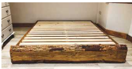
10 Bed in position and slats installed, with middle strut provided
