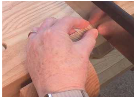
20 I use a 'pinch' grip to position the saw at the start
