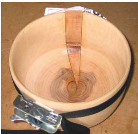
50 The pearwood patch is glued into the recess
