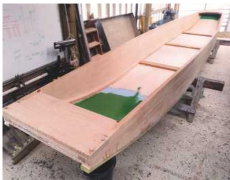
5 The shell, now formed, can have the jig removed and still retain the shape. Ready for fitting out with seat backs, knees and deck
