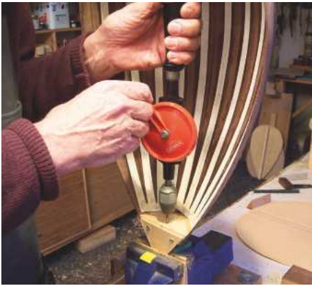
18 A hole is drilled ready to receive the screw that will hold the neck to the bowl
