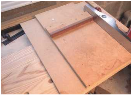
4 A simple shooting board will make accurately squaring the ends of timber (among other tasks) quick and easy
