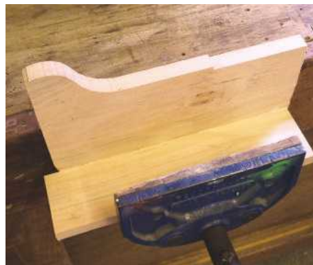
8 The first stage of building up the front wheel arches/housing
