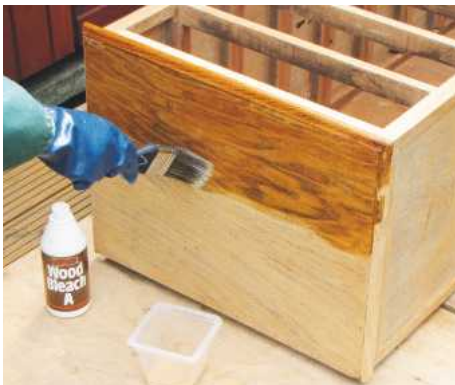
9 When sanded, brush on the activating solution and allow to dry, then apply the bleach in the same way
