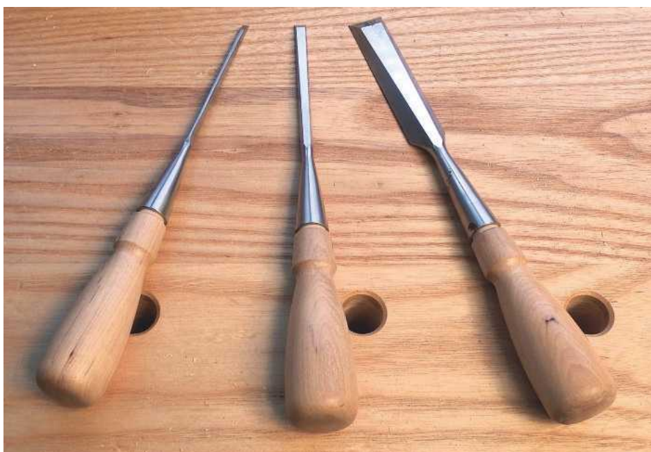
14 Cutting back to the shoulder-line is a critical task in dovetailing. A few good bevel-edged chisels will make it much easier
