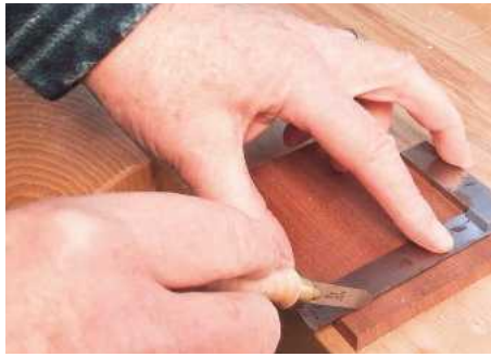
5 A cut line is needed to mark the shoulders. A simple square and a knife will get you started. However...
