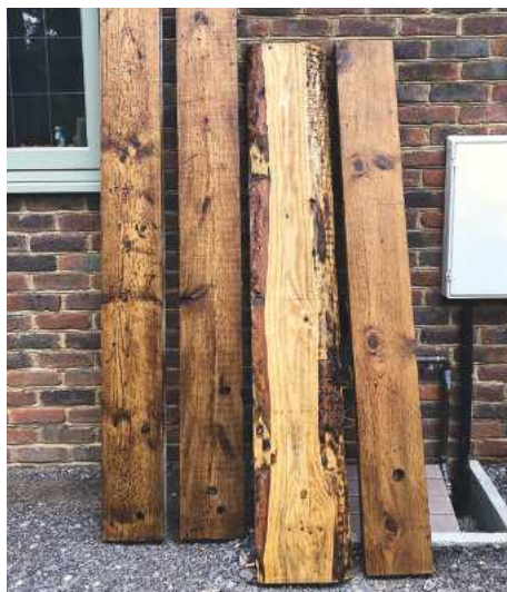
8 All beams waxed and drying
