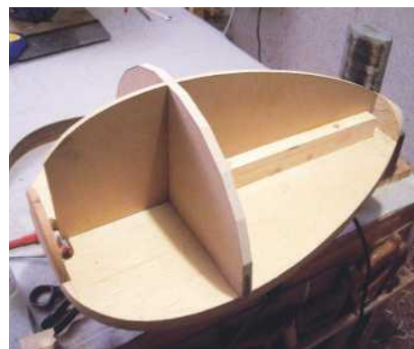
5 The former assembled with tail and neck blocks in place
