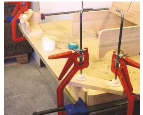
9 Another section is added to the front wheel arch
