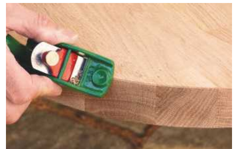
The Kunz is a handy little tool for detailed work, such as decorative chamfering
