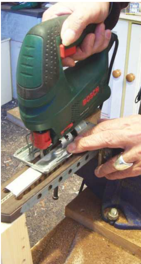
27 A jigsaw cuts out the string slots with ease
