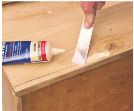
8 Fill any cracks or blemishes with matching filler and sand back when dry; this may need tinting later
