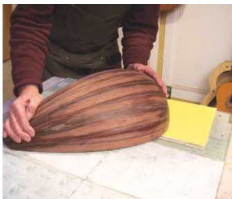
13 Ensuring the outer rim of the bowl is dead flat
