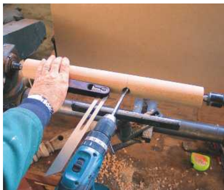
36 Bore the rail socket first
