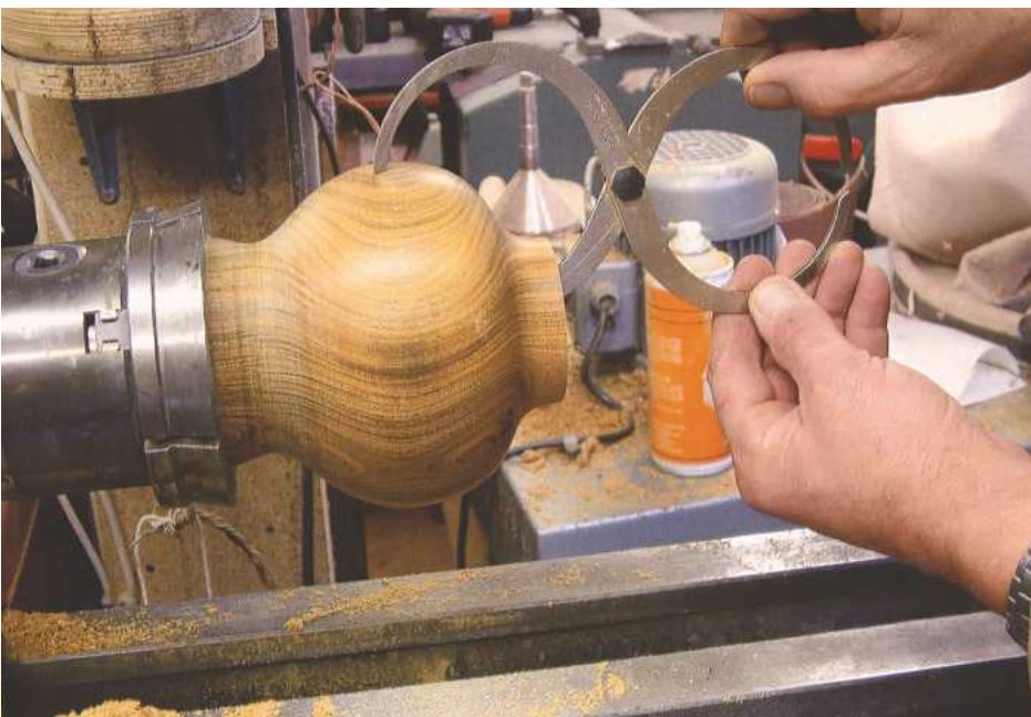
6 Use callipers to check the wall thickness
