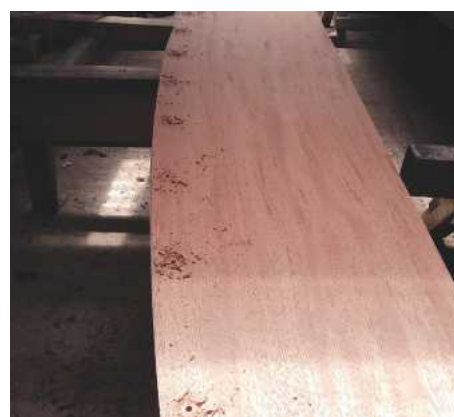
1 Sides are pre-drilled ready to fit the chine
