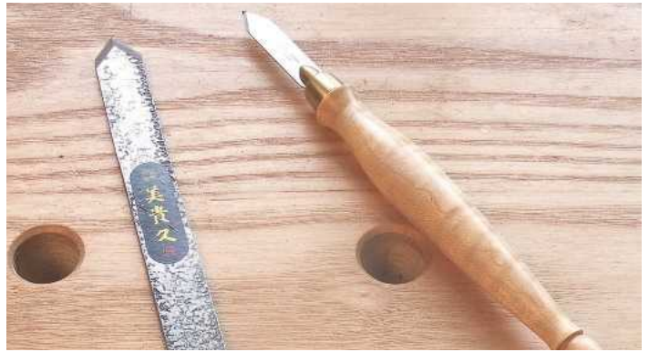
17 These double-bevel knives are excellent for most basic dovetailing
