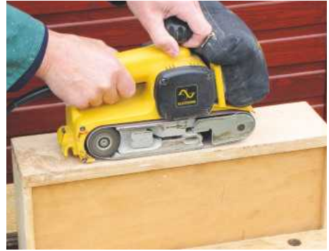
5 Although a belt sander can be pretty aggressive it's a great tool for cleaning up wide, flat areas...
