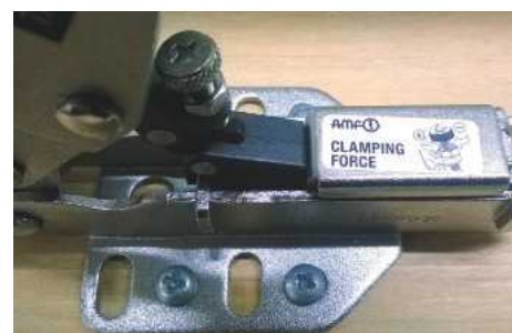
Adjustment screw and clamping force lock mechanism
