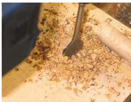
21 Making the recesses with a flat bit
