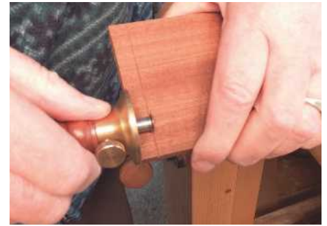
6 ... as they run parallel to the ends, a gauge is simpler, quicker and less error-prone
