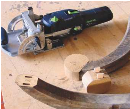
7 The Domino joints once cut
