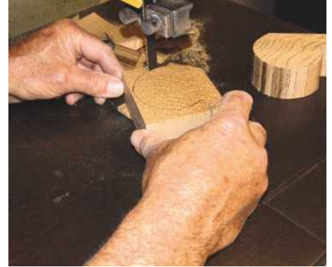
6 The replacement ends cut out on the bandsaw
