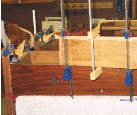
4 Gluing these replacements onto the sides
