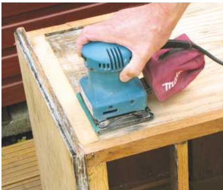
6 ... while a palm or detail sander is ideal for getting tight into corners; you'll still need to do some hand sanding, though
