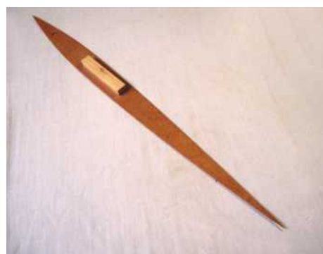
8 The rib template ready for use
