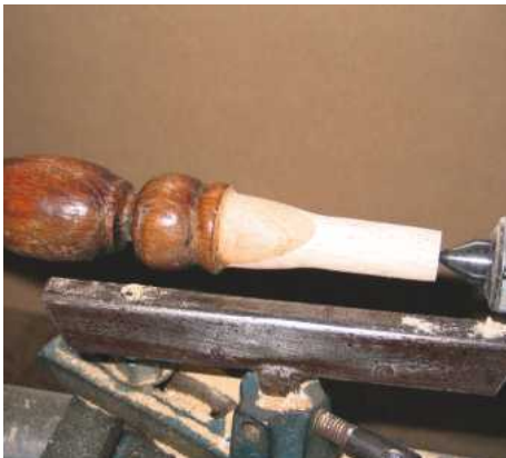
10 The new spindle end is turned
