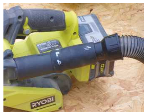
A rubber adaptor enables the hose to be fitted to a power tool with suitable dust port, though there's no on-board storage for this
