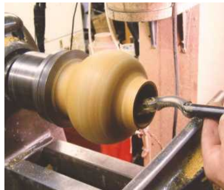
5 Hollow out the container. Stop the lathe occasionally to clear the shavings
