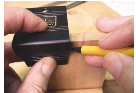
9 The simpler the operation, the less chance of error. This 'saddle' marker from Veritas lets me mark the end and face lines in one go. I love it!
