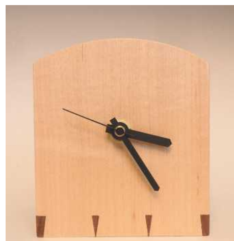
2 The 'London' dovetail has pins tapering to a single saw-kerf. This is more fiddly than a basic dovetail but also, I think, more elegant
