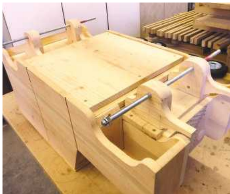
16 The assemblies are roughly positioned to see if they fit
