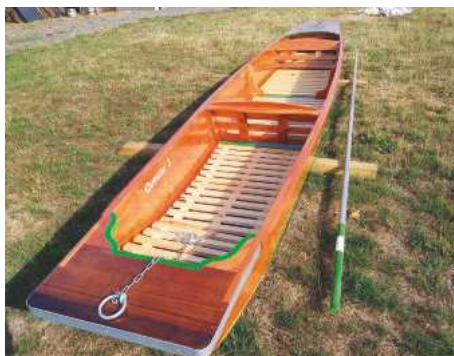
12 Awaiting delivery. Punt painted and varnished as described in text. Eye bolts and steel bumpers attached to the ends
