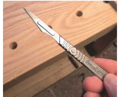
18 However, for very fine dovetails, only a scalpel is fine enough to slip into the space available
