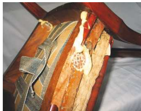
43 Expanding polyurethane glue will fill the spaces
