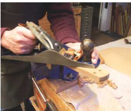
22 Tapering the peghead with a No.5½ plane
