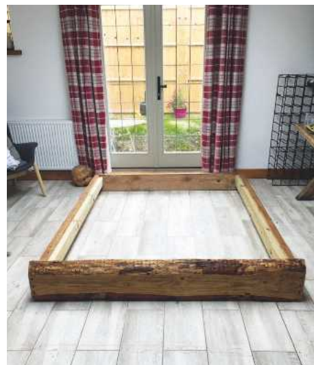
9 Bed frame constructed: four beams bolted together
