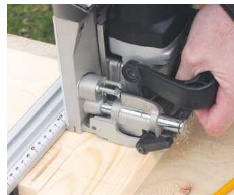
3 Mark out positions for biscuits on the side and end components. Cut the slots for No.20 biscuits
