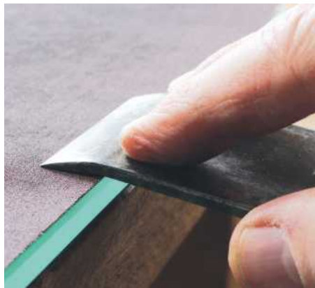
28 Working the cap iron on a piece of emery cloth on plate glass
