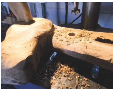
18 Drilling a hole into the neck using a Forstner bit, ready to accept the handle bar
