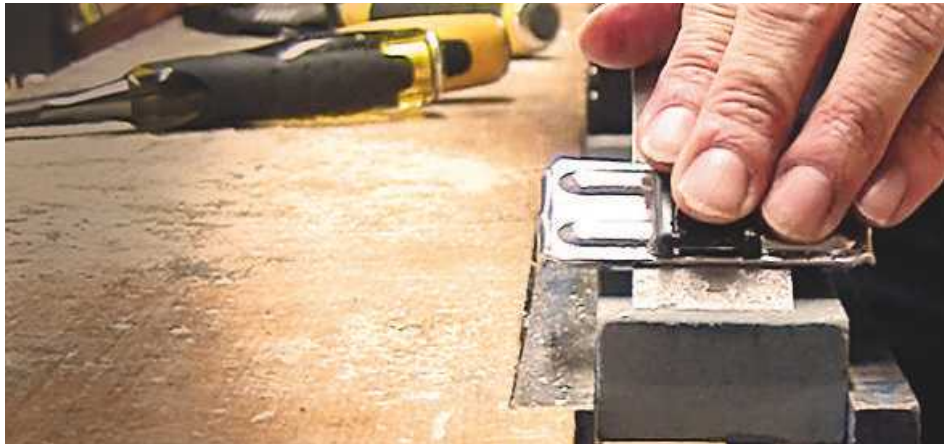
9 Sharpening a chisel on an oilstone using a guide
