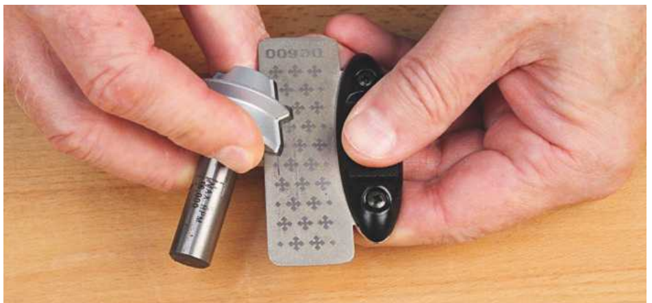
10 Sharpening a router cutter with a diamond slip
