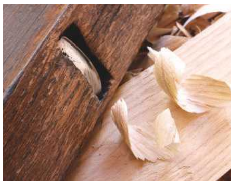
3 ... with a narrow heavily cambered iron
