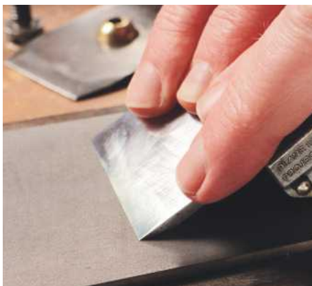
29 Honing the iron on a diamond plate...
