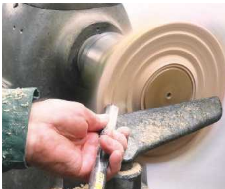
16 Remove the waste from the wings in steps until...
