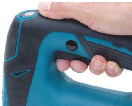
Located centrally, the large on/off trigger enables you to use it with two fingers nestled underneath
