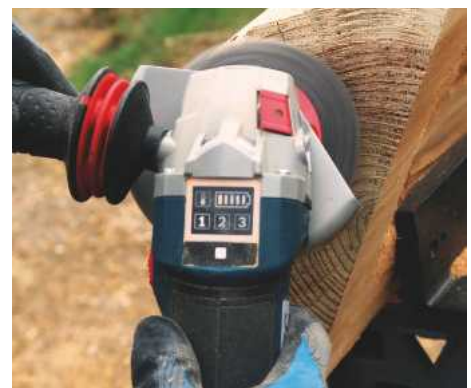
The light indicator showing low battery power
