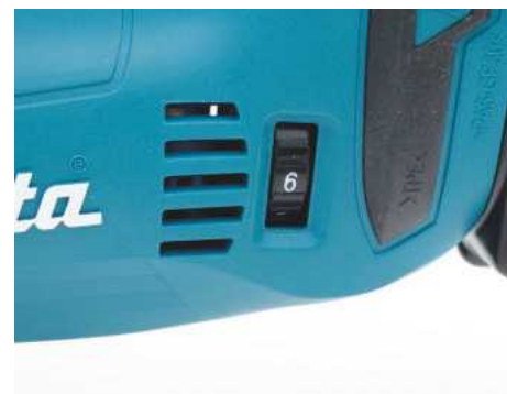
Towards the rear the ridged speed adjuster dial is easy to use while sawing, though it's only visible from one side
