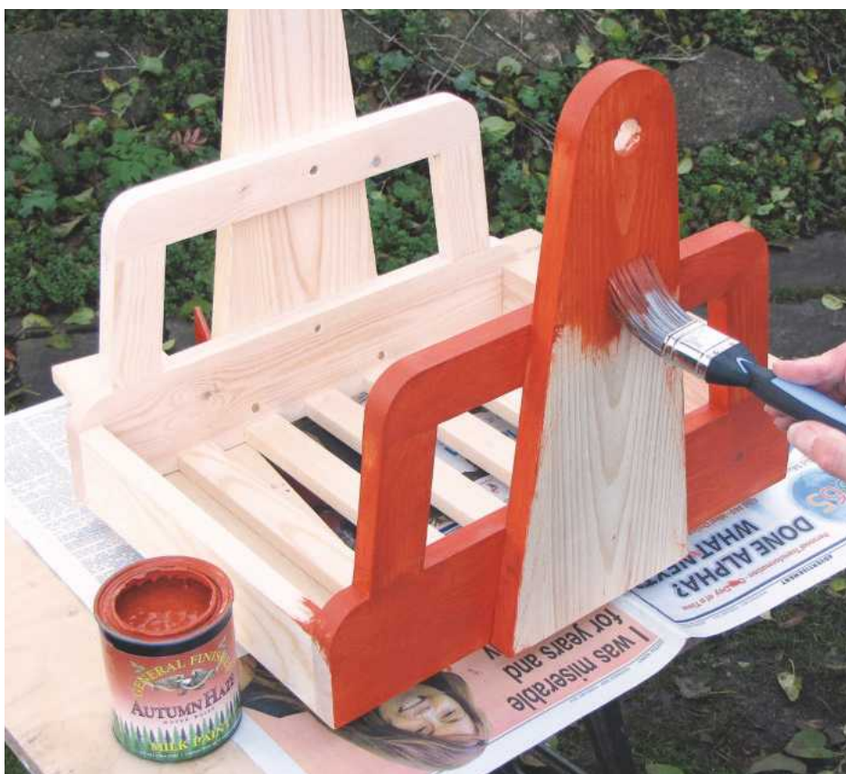
24 Fill any holes and sand the box. Brush on a couple of coats of varnish or a suitable paint
