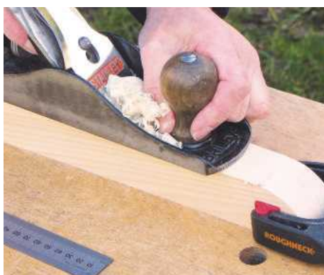
10 Cramp both sides together and grip them in the bench jaws. Plane down to the pencil lines
