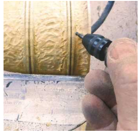
21 To get close to the small beads I changed to a small grinding burr. I textured the whole surface trying not to leave any flats; these would be created by sanding later in the process
