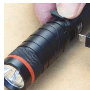
The Micro USB plug is a tight fit into the port on the torch, revealed by lifting a rubberised flexible flap
