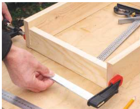
5 Assemble the box and add cramps across the ends. Check for square and adjust if necessary
