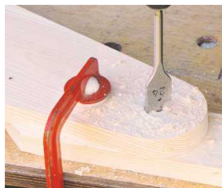
12 Drill holes for the handle using a 24mm flatbit. Check the fit by drilling an offcut first
