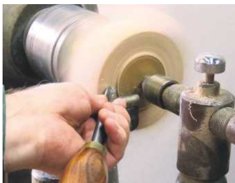
22 Mount the lid between centres to cut a spigot
