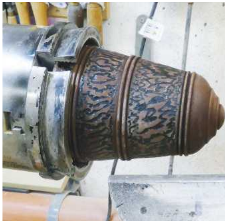
26 This bell was slightly smaller in diameter than the first one, so I remounted it by holding it in large Axminster Gripper Jaws. The sharp edge on the rim of the bell fitted perfectly in the groove of the jaws
