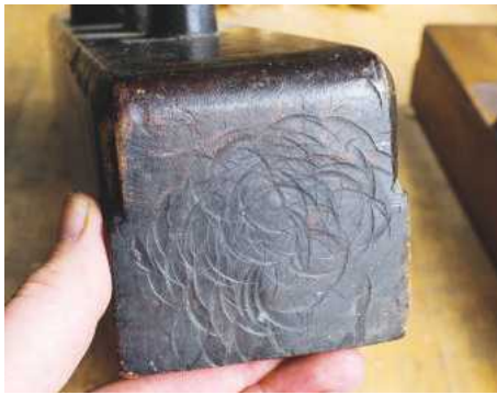
19 Historic hammer marks on the heel of the trying plane
