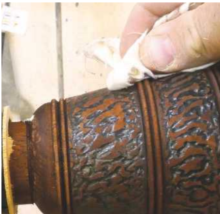
25 I applied water-based brown stain to the outside of the piece. Because the stain is translucent it will not show up on the black, which means it will only stain the exposed natural wood
