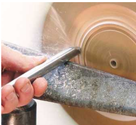
14 Use a bowl gouge to cut a cove next to the step...
