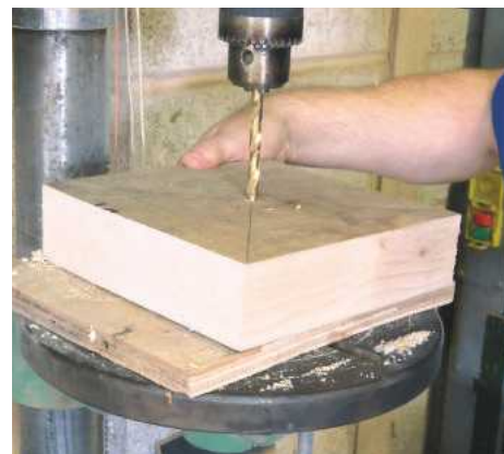
3 An 8mm hole is required in order to mount it on a screw chuck
