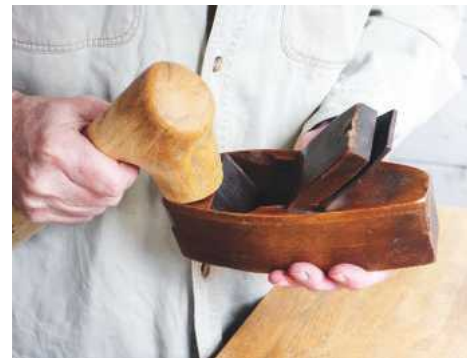
20 A light knock on the toe retracts the iron a tad, sometimes
