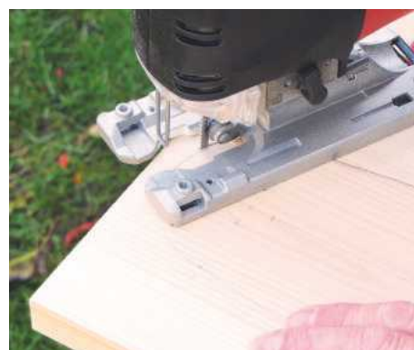
9 Cut out the tapered sides carefully using a jigsaw. Alternatively, do this with a bandsaw
