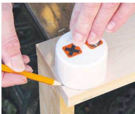
7 Draw around a suitable object to find a pleasing radius to shape the top edges of each side
