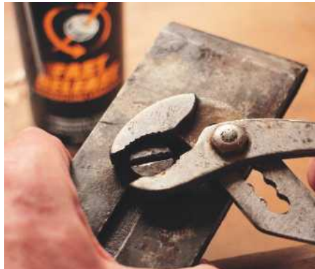
26 PlusGas and waterpump pliers release a seized iron...
