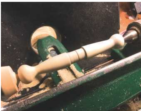
16 The tulipwood offcuts mounted on the lathe
