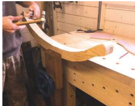
21 ... and being shaped with a spokeshave (after being screwed together)
