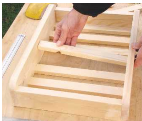
14 Saw the base slats so they are a snug fit in the box. Lightly sand the arrises before fixing
