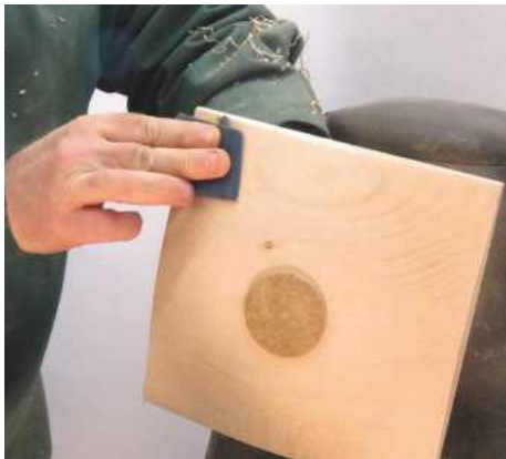
10 It is safer to sand and polish the corners with the lathe stationary
