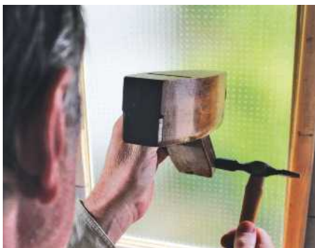
23 A sideways tap of the hammer levels the iron
