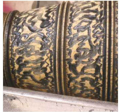
24 Sanding the outside of the piece allowed me to remove the paint on the high points. I made sure the paint was very dry – it's best to leave the piece overnight if possible
