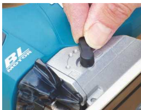
There's a four-stage pendulum selector button on the side of the cast alloy gear housing
