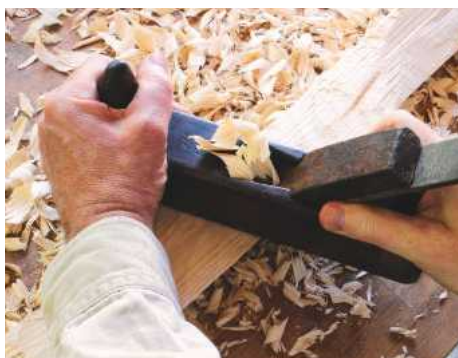
2 The scrub plane works a split ash bough...
