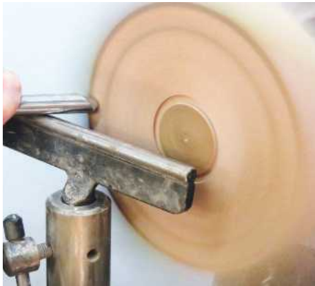
7 Shape the outside ogee using a combination of the pull cut...
