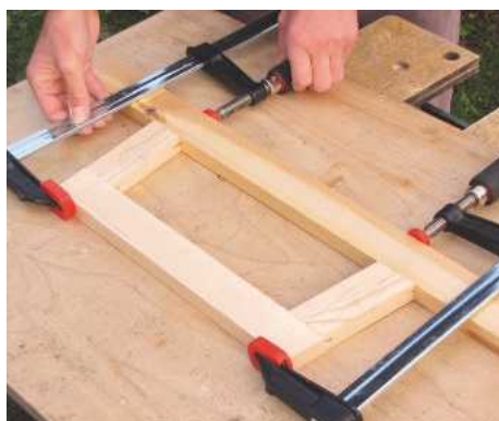
19 Cut biscuit slots and glue together the top rails and supports. Shape the ends when dry
