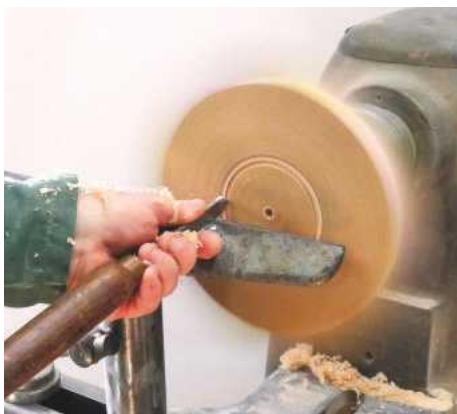
13 ... and use a parting tool to cut a step
