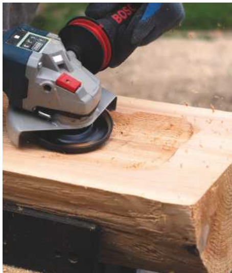
The Bosch angle grinder works brilliantly for woodcarving when fitted with a TurboPlane accessory
