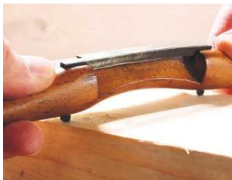
16 Pushing out the iron for honing
