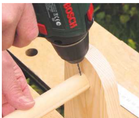
23 Slide the handle through the holes. Drill pilot holes at each end and fix with lost-head nails
