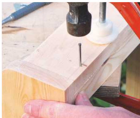
16 The two outer slats are butted up against the ends. Glue and cramp in place before nailing
