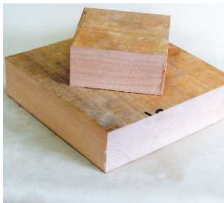
2 The base of the 'box' is a 200mm square and the lid is 100mm square
