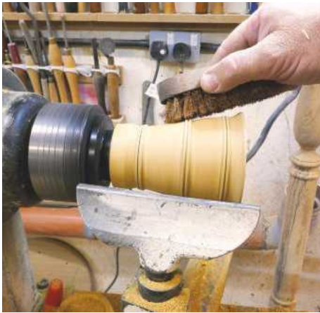
22 Whenever you do any texturing you are likely to end up with fluffy bits that need removing. A drill-mounted brass or plastic brush is often required, but on this timber, I could get away with just using a brass liming brush
