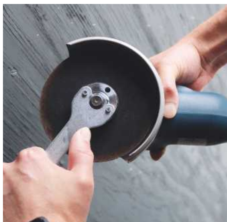
Changing the cutting/grinding accessories using the supplied tool
