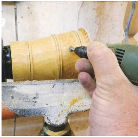
20 The second iroko bell was turned in the same way, but I decided to add a little texture to the piece. The ball cutter from Henry Taylor's Decorating Elf works perfectly in the Proxxon mini drill
