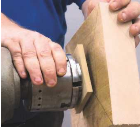
4 Here I am using a spacer on the screw to limit the depth
