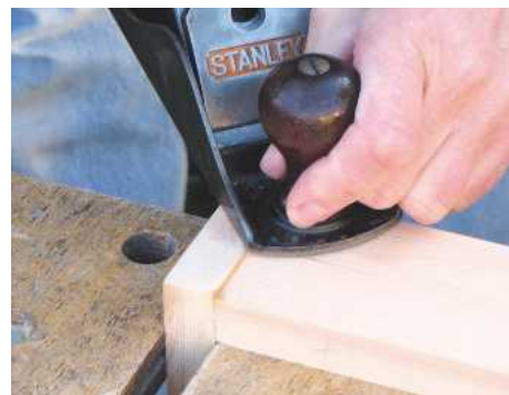
6 When the glue has dried, trim the excess end-grain carefully with a bench plane
