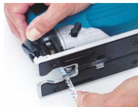
Pushing a spring-loaded, clear plastic lever at the front with your thumb opens the blade mechanism
