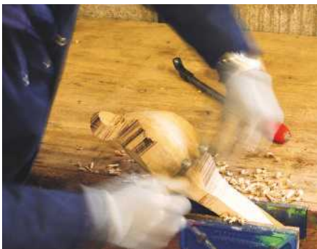
8 Most of the shaping is done with a spokeshave
