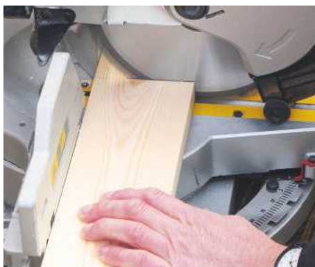
2 Cut timber to length for the sides and ends. Allow an extra 2mm on each side piece
