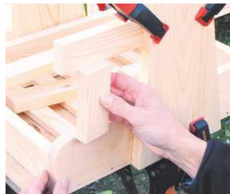
18 Cut the rails that make up the upper sides. These are butt jointed together with biscuits
