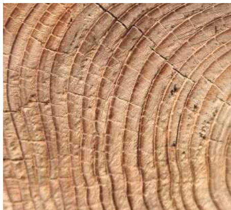
Weathered end-grain texture created using a wire brush fitted in the angle grinder
