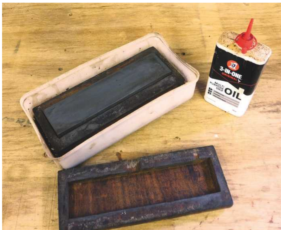
1 My double-sided oilstone in a wooden case with a plastic container to retain any oil seepage
