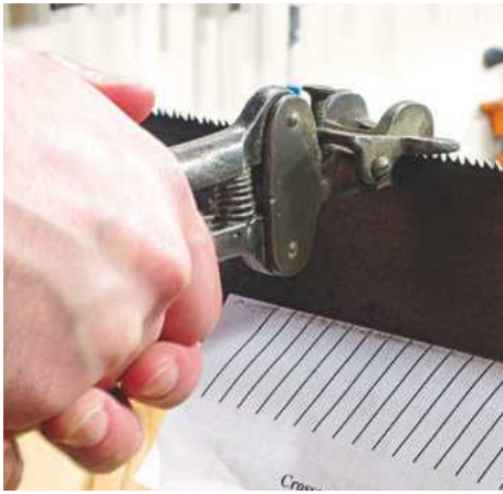
8 Using a special tool to set the saw teeth
