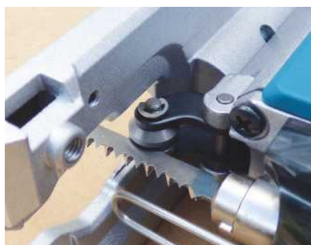
Attached to the housing is a substantial steel roller mechanism, which supports the blade well
