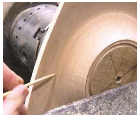
18 Blend the steps into the right-hand side of the cove
