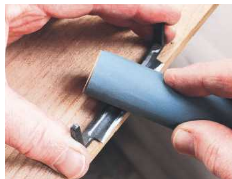
17 Using fine abrasive around a wooden former
