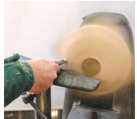
9 ... completing the shape with a shear cut going with the grain
