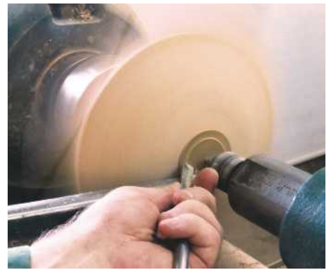
33 ... to remove the chucking spigot
