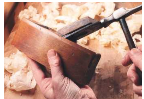
21 Fingertips monitor projection while the iron is tapped
