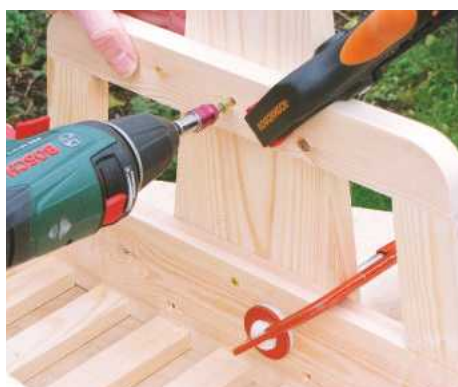
22 Screw the tapered side pieces to the inner rails and box from the inside. Don't glue these, though
