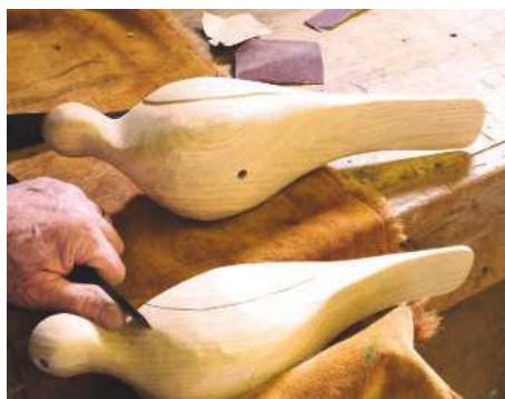
10 Marking on the line of the wing detail carved in each side
