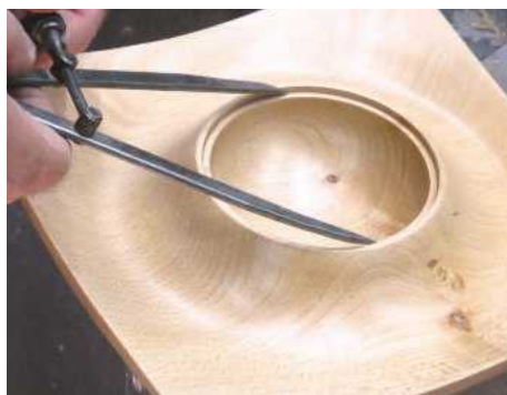
23 Measure the diameter of the step...
