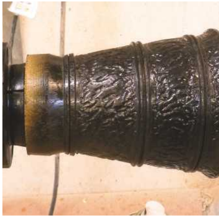
23 After giving the timber a coating of acrylic sanding sealer, I sprayed the whole of the outside with ebonising lacquer. I was careful not to get any of the black inside the bell
