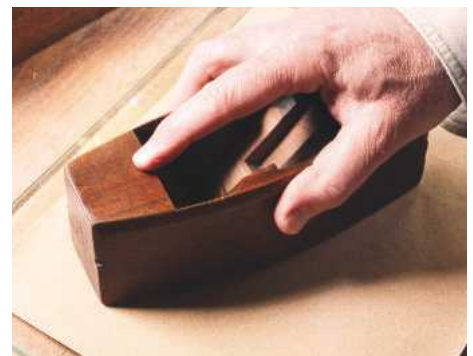
24 Flattening the sole with sandpaper on plate glass
