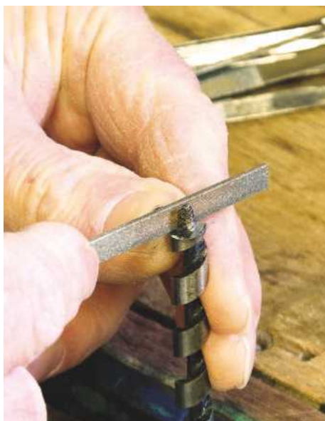
6 Sharpening a spur bit with a micro file – more in the background
