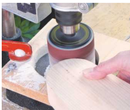
11 With the sides still held together, shape the top curve using a sanding drum mounted in a drill
