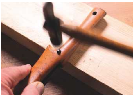
14 ... while tapping on the iron's tangs to open the mouth...
