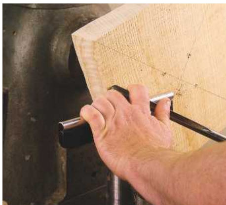
1 This type of grip is not recommended, particularly when turning pieces that are not round
