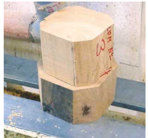
27 Last but not least was the elm bell. To achieve the size, I needed to make it in two pieces. I cut the timber off to ensure it was the right size, so the join would be hidden by a bead detail on the outside of the bell
