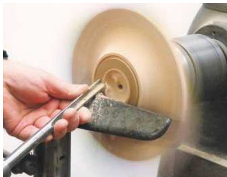
20 Hollow the box using a bowl gouge
