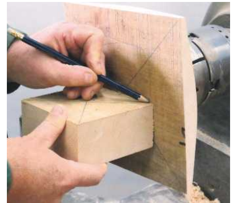
12 Mark the diameter of the box section...
