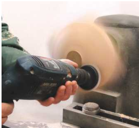
11 If you choose to power sand, ensure to keep the sanding disc as upright as possible
