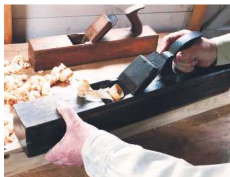
8 Fingers under the sole keep the plane on track
