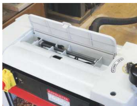
A useful compartment on top holds the blade setting jig and tools
