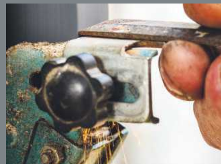
2 Grinding back the edge to remove chips and dinks, sometimes caused by hidden nails, or someone using it to open a paint tin
