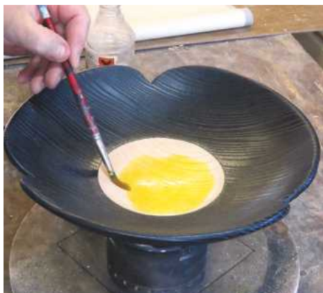
24 Apply spirit stains and blend the colours together
