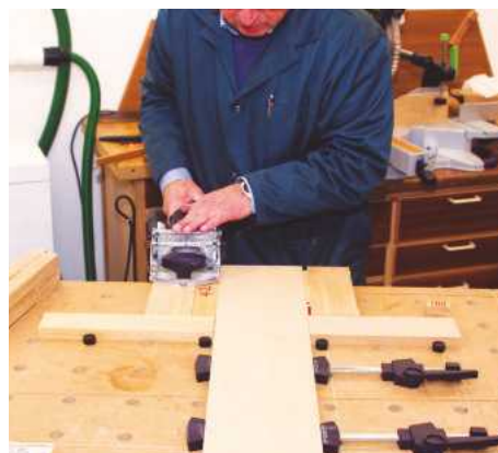
2 Jig work on the MFT3
