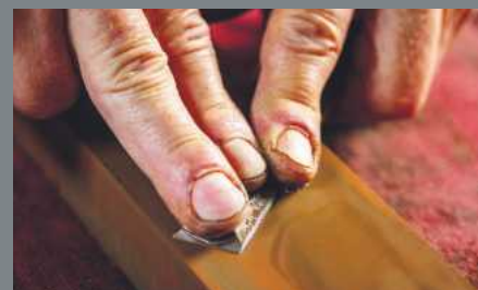
5 Flattening the back on a 1,200 grit waterstone. Make sure the chisel is pressed flat on the stone's face, and rub it along the length of the stone. If your pressing fingers become exhausted, you can hold a piece of wood along the back of the chisel to help maintain an even pressure
