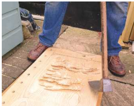
17 Initial shaping using an adze
