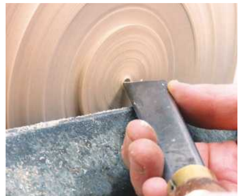
6 Use the point of a skew chisel to cut a pop mark in the centre of the spigot
