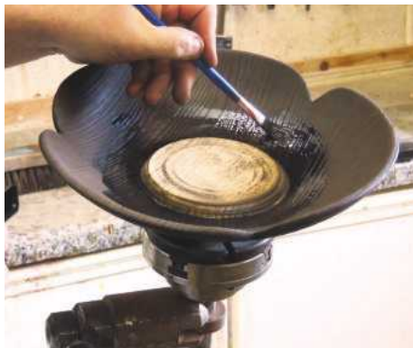
21 Brush off any carbon and paint the scorched area with acrylic dye
