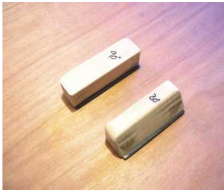
69 Home-made fret edge trimming tools
