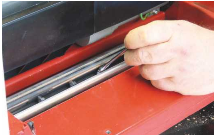
The bolts securing the blade holder were very tight – use a good spanner
