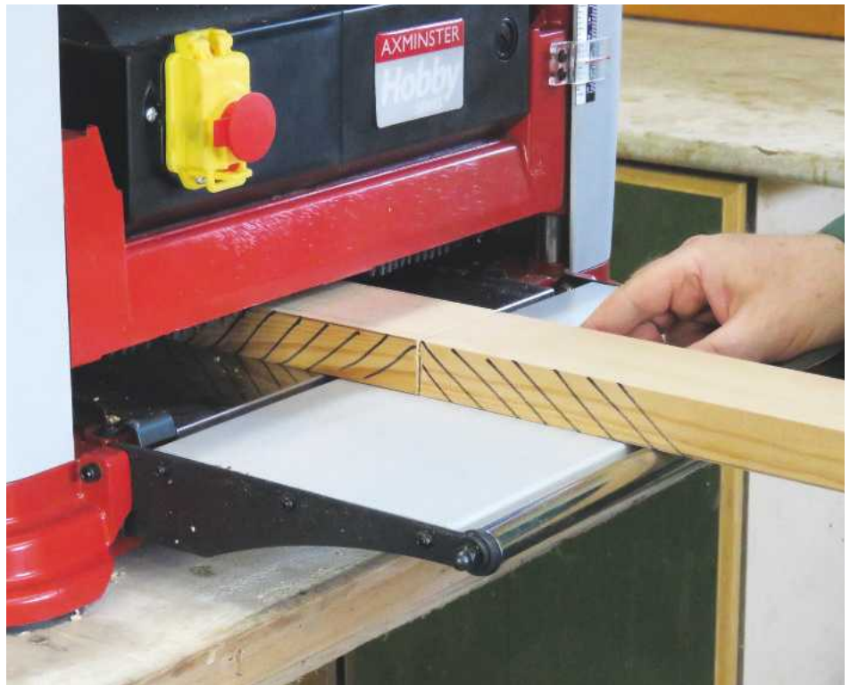
5 Feed stock through the machine so that the pieces are butted up against each other
