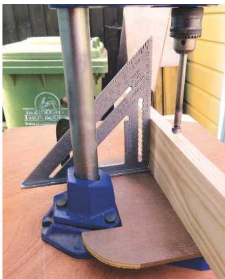
11 Keeping the crest rail vertical while drilling
