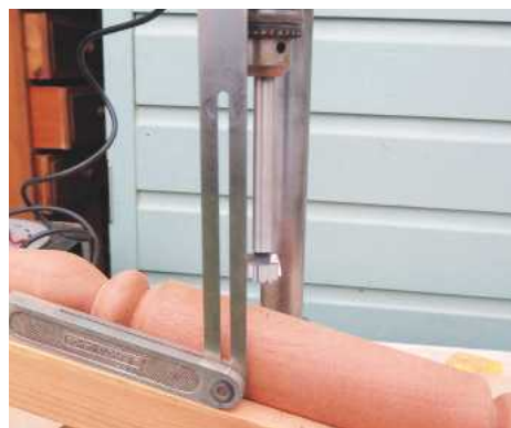
13 Drilling outer uprights in the cradle
