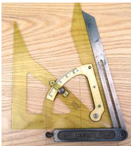
8 Transferring the 12° angle to a sliding bevel
