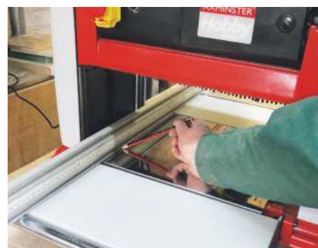
Close any gap here by adjusting the in- and outfeed tables...
