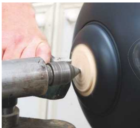
25 Reverse chuck the bowl to remove the chucking spigot
