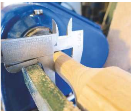
6 Checking spindle diameter
