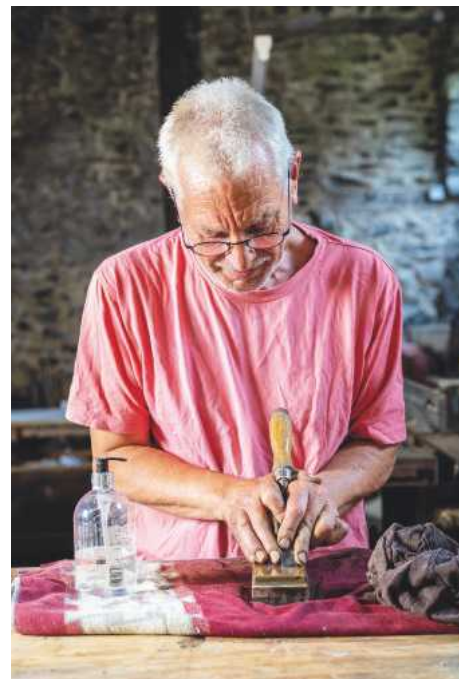
5 Try to use yourself as a jig. Keep your elbows locked and rock back and forth from the hips. Your hands and forearms move as rigid supports for the chisel and really keep it at the desired angle
