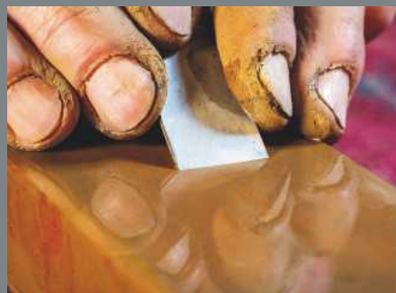
6 Place the chisel on the stone so that it rests on the grinding bevel, then lift the handle 5^\circ ; this is the honing angle. Hone the edge by rubbing the chisel back and forth along the stone
