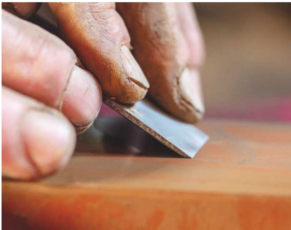
4 I like to cross my thumbs on the back of the chisel and press down lower on the blade with the first two fingers of both hands. I find this helps to keep the chisel angle constant
