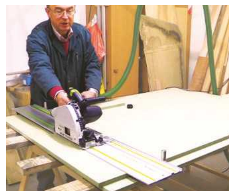
4 Simple track saw cutting station in use
