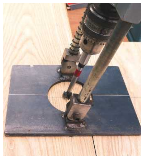
9 Drilling spindle holes using an angled drill guide
