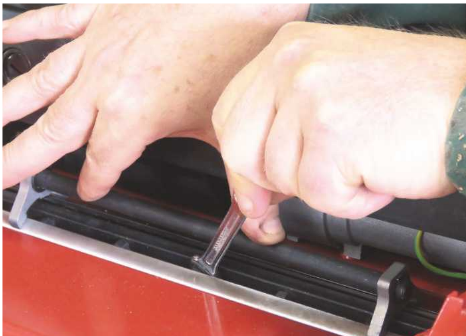
The blade alignment jig is quite easy to use
