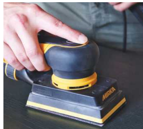
Sanding between coats of finish
