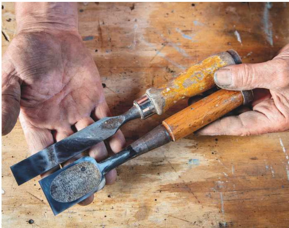
2 A western and a Japanese chisel. The Japanese tool has been manufactured with a hollow ground back, which makes sharpening faster
