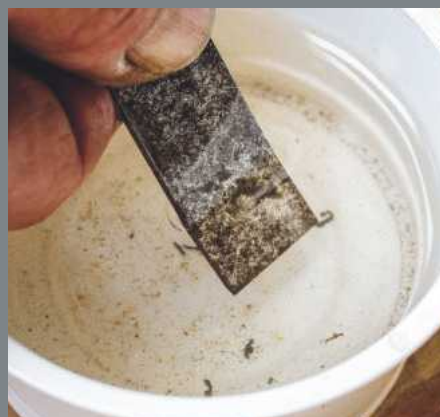
4 Quenching the chisel during grinding. If the tool gets hot enough to discolour to a bluish shade, it means it has lost its temper and has become weaker. Quench often to avoid this
