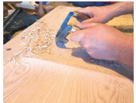
18 Hollowing out using an inshave
