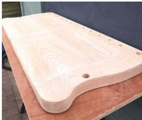
20 Detail of seat end after shaping
