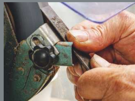
3 Grinding the main bevel. The toolrest is set to produce an angle of approximately 25^\circ . The curvature of the wheel means the bevel will be hollow ground
