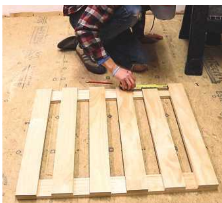
5 Finding the centreline of the horizontal board and measuring out from the centre in each direction
