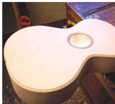
60 Binding and purfling channels in the front
