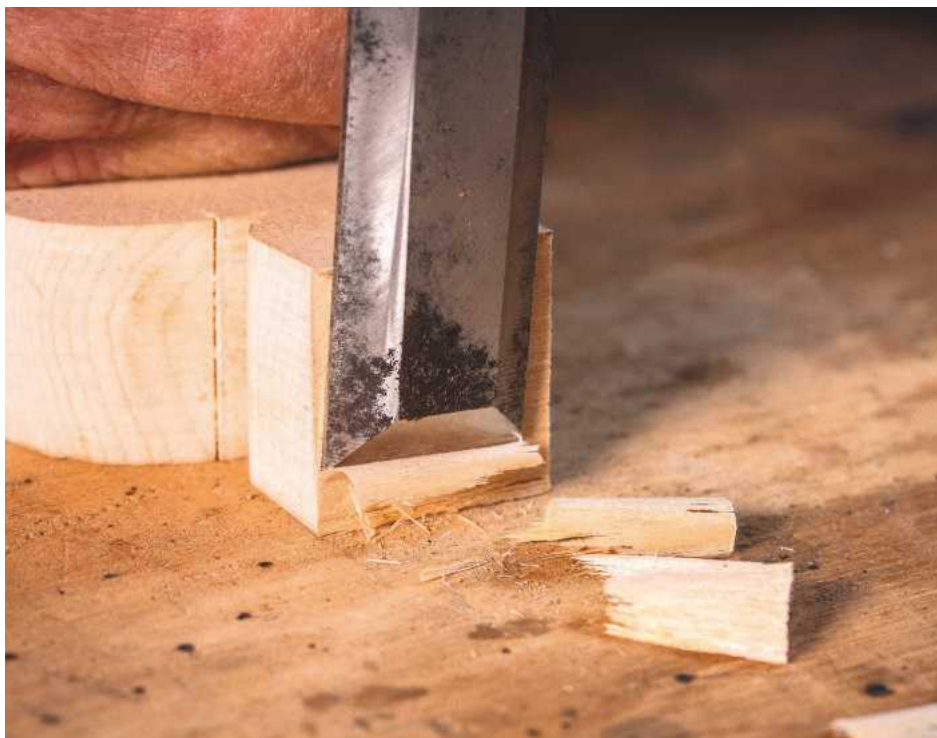
6 Check your sharpening by paring some hardwood. This bird's eye maple comes off in smooth, controllable slivers
