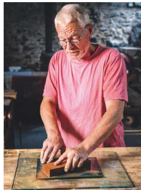
3 Flattening a waterstone using a piece of plate glass and wet and dry paper. Keep everything well wetted and rub the stone back and forth until it is flat again
