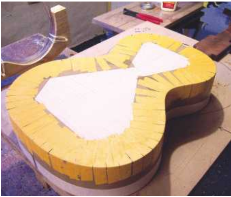
62 The bindings held in place on the back with strong masking tape
