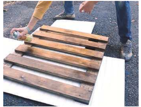
9 Applying two coats of spray shellac once dry
