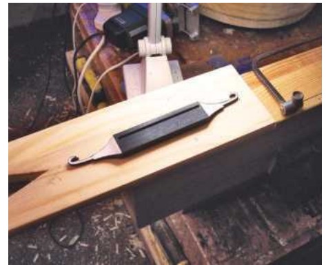
70 The bridge roughly made showing the saddle slot
