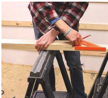
2 Marking out one of the boards...
