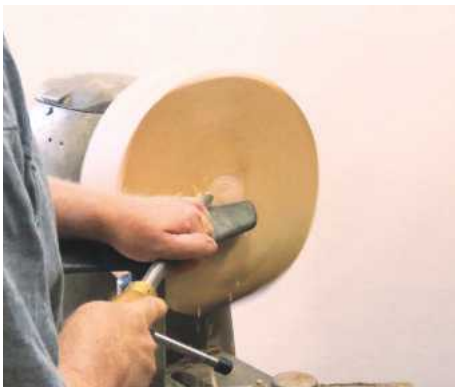
1 Use a pull cut to flatten the bottom...
