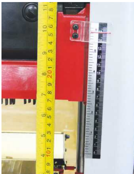
A mismatch between the actual height and what the scale reads
