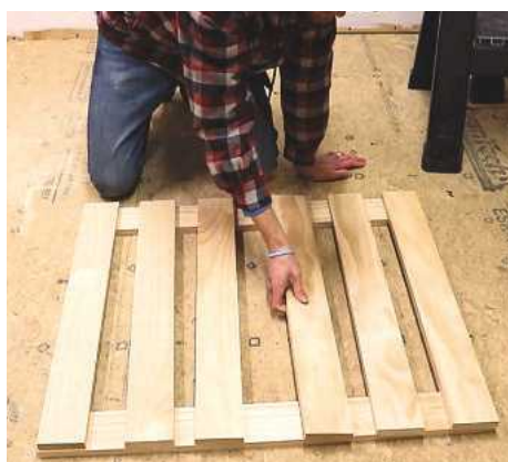
4 Laying out the gate components before assembly
