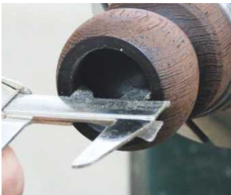
16 Measure the internal diameter of the threads...
