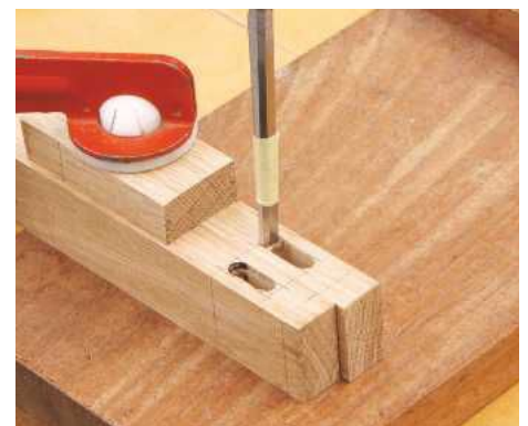
30 Rout mortises to depth and proceed to square up the ends with a chisel. Use masking tape to indicate overall depth
