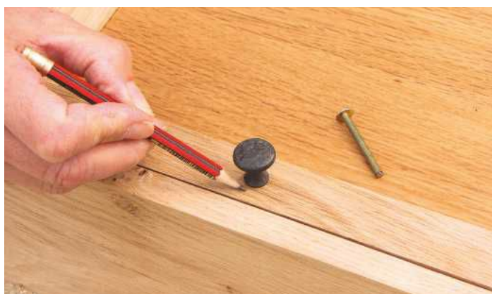
41 Position the door knob slightly above the middle of the cabinet. Drill for the bolt and cut this to length if necessary
