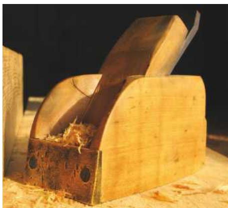
30 A brass plate protects the blade
