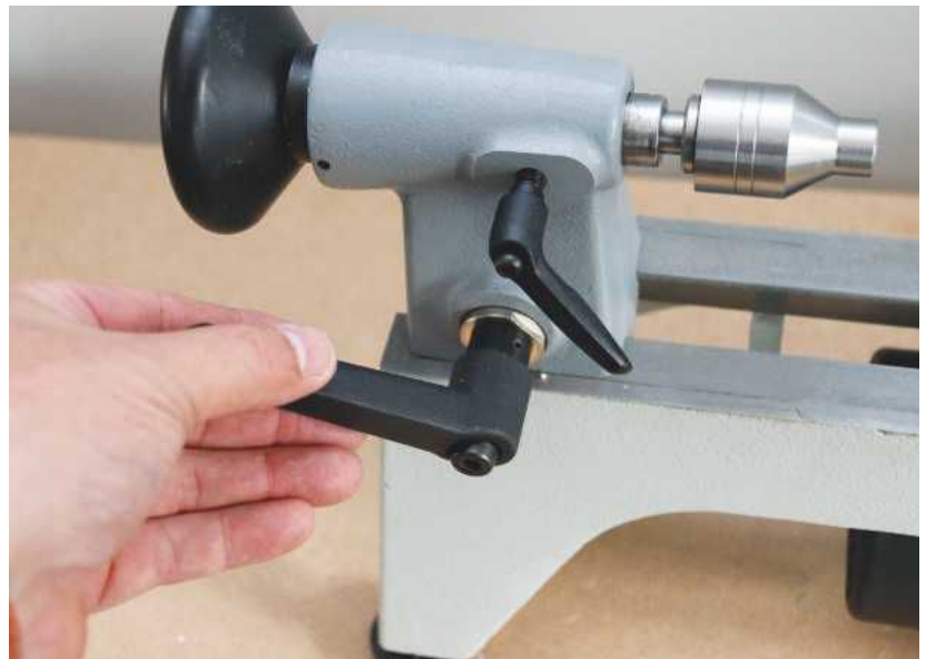
The tailstock locks off with a good quality large lever at the rear side
