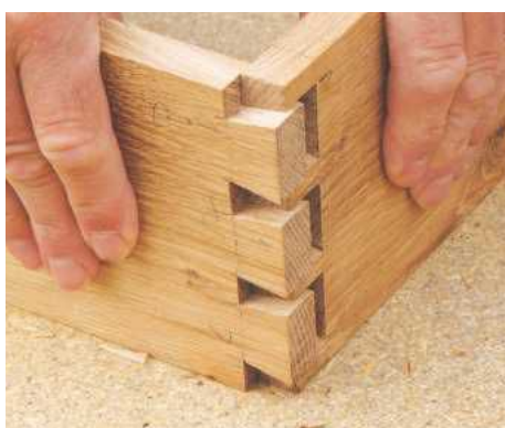
16 Lightly tap each corner joint together (about 2mm) and check where tails or pins need trimming back
