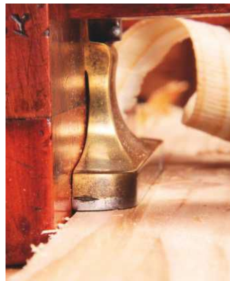
28 A dovetailed boxwood insert has withstood heavy use
