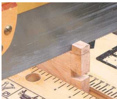
11 Saw the outer shoulders neatly with a dovetail saw, keeping the tool square
