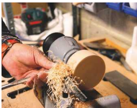
Small bowl-type jobs can be carried out using the screw chuck and faceplate
