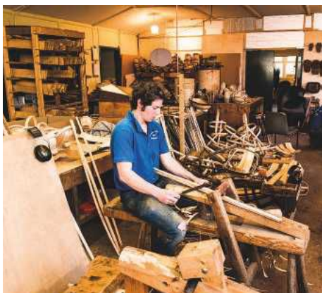
12 Shaving the handle and rim to the required width and thickness
