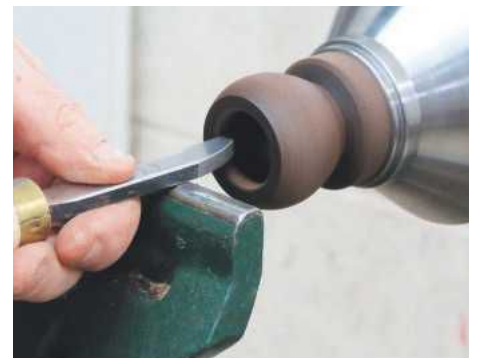
15 Cut the female thread after polishing the inside of the box
