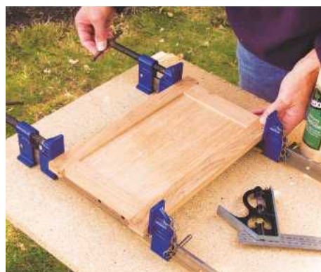
36 Make sure the panel is not too tight in the groove when cramped. When gluing up, try to avoid gluing the panel
