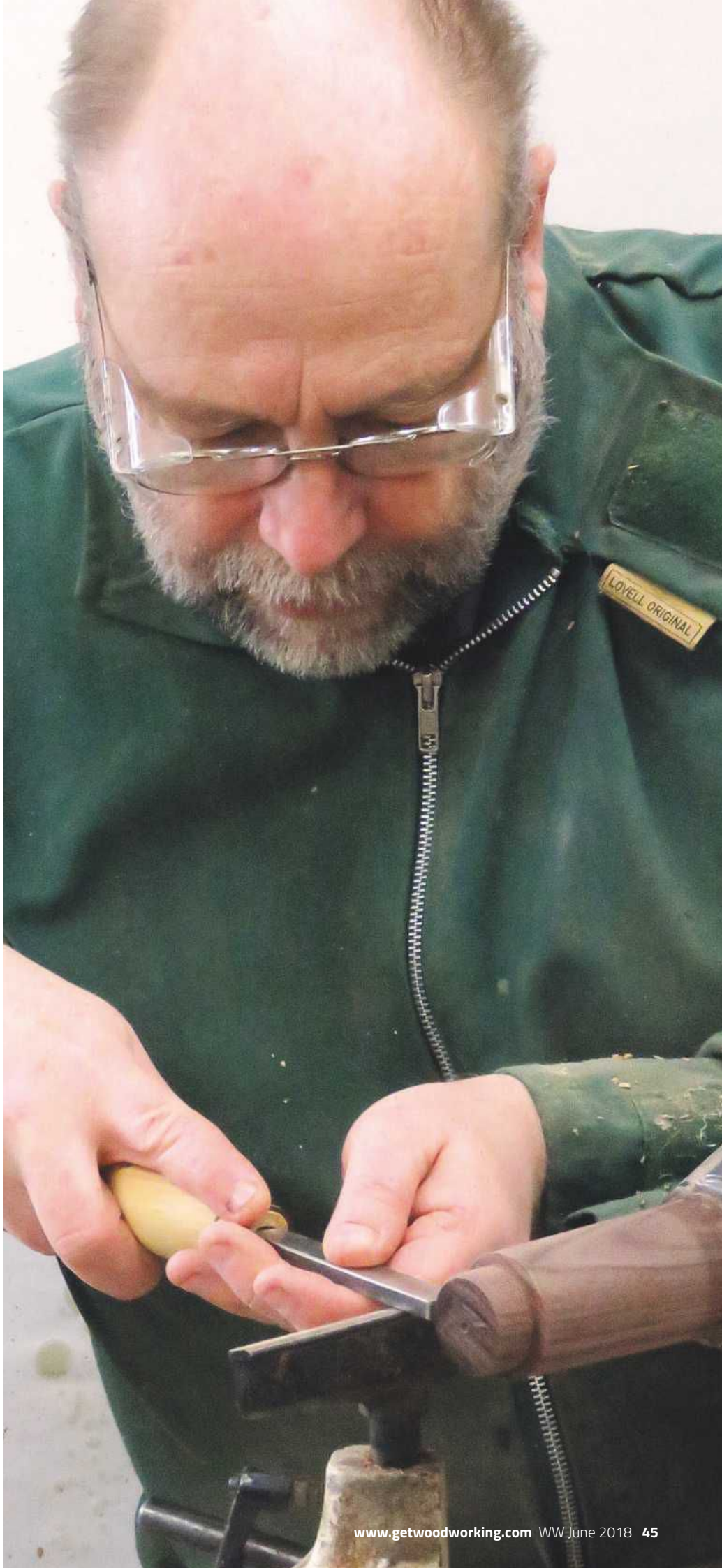
8 Male threads are normally cut on a tenon. Note the relief groove...
