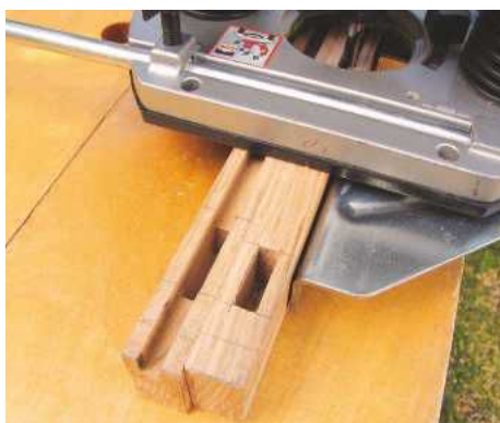
31 With a 6mm straight cutter, rout a groove along the inner edges of rails and stiles. Stop this short of the ends on both rails
