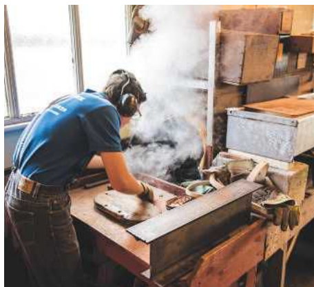
13 The shaved pieces are put in the steamer for about 15 minutes
