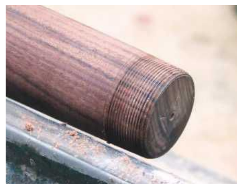
7 Allow the chaser to follow the spiral to complete the thread
