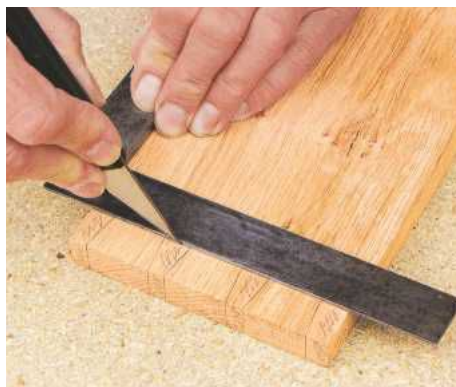
8 With the point of a marking knife, scribe shoulder lines across each of the ends. Alternatively, use a cutting edge
