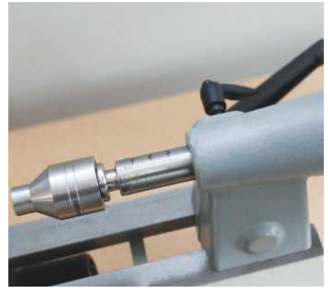
The tailstock features a graduated scale, which is particularly useful for blind drilling jobs
