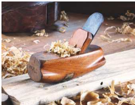
12 The bollow's sole is rounded both ways
