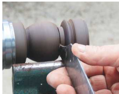
14 Roughly shape the box then part the lid from the base
