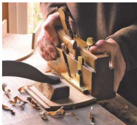
22 Moving fillister cutting a rebate in elm
