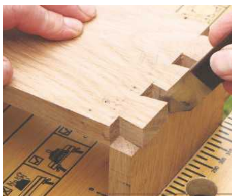
13 Clean up the tails with a chisel, then lay the tail piece on the corresponding timber. Carefully mark the pin positions
