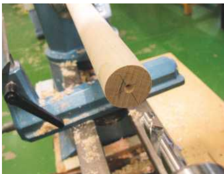
Pilot drilled hole to start auger
