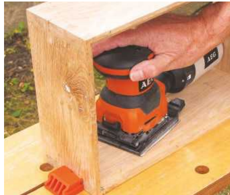
26 Fill knots and splits with stopper such as Mohawk (Behlen) epoxy putty. Sand interior surfaces before fitting the rear panel
