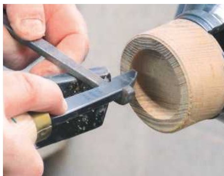
2 Using an armrest means you don't need to move the toolrest
