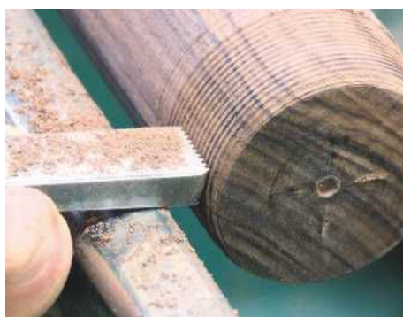
6 As the thread gets deeper, swing the tool round to 90°
