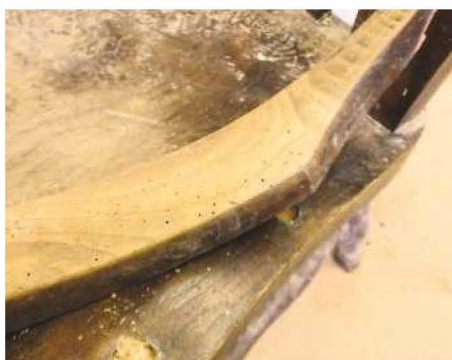
2 A close-up of the wormy arm shows the extent of the damage
