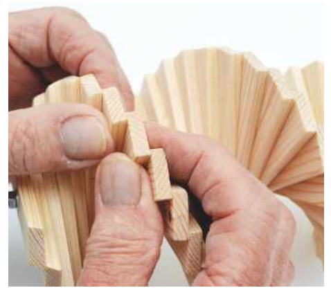
12 Use your fingers to twist the pieces round the rod so that they overlap slightly (think spiral staircase!)
