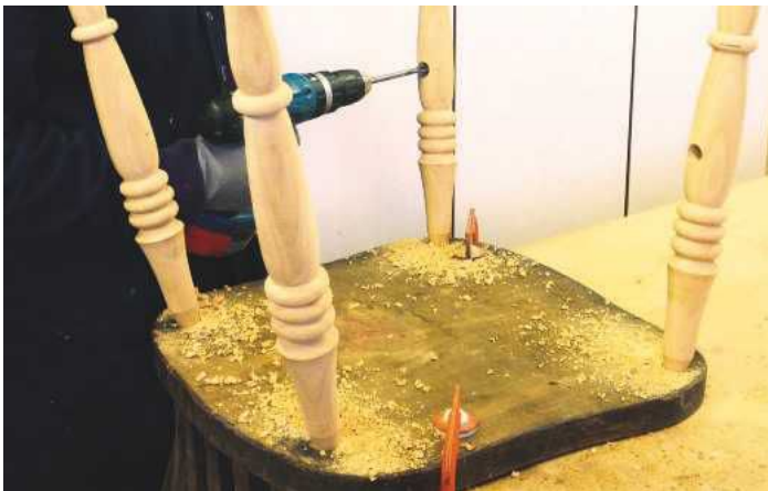
15 Freehand drilling of the socket holes
