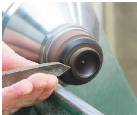
19 Take a small shaving off the peaks of the threads and re-chase
