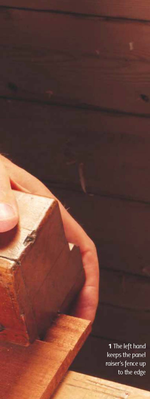
6 Hollows for thumbs in the boxwood guides
