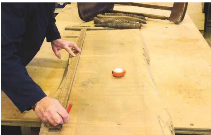
8 Cherry wood for the replacement pieces. Marking a straight edge on the wane to start
