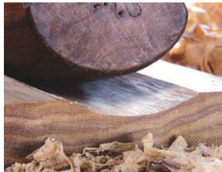
13 Friction is greatest in front of the blade
