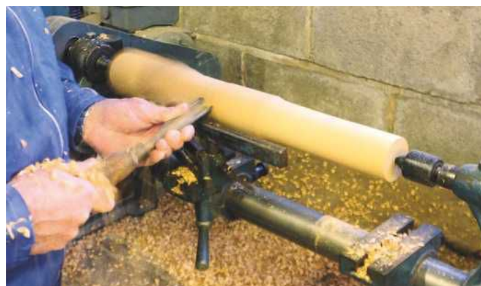
11 All the turned components were roughed down before the profiles were defined
