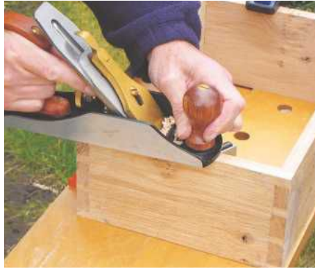
20 Next, true up the front and rear edges of the box, checking this does not rock when placed on a flat surface
