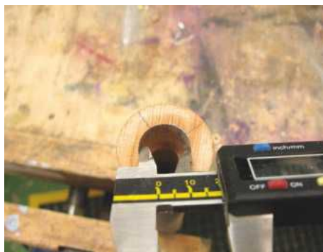
Checking socket measurement
