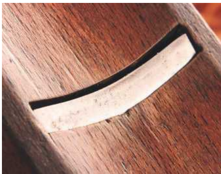
8 The blade and sole are concave
