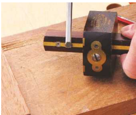
28 Adjust the mortise gauge pins to the chisel you'll be using. Mortises should be central on stile thickness
