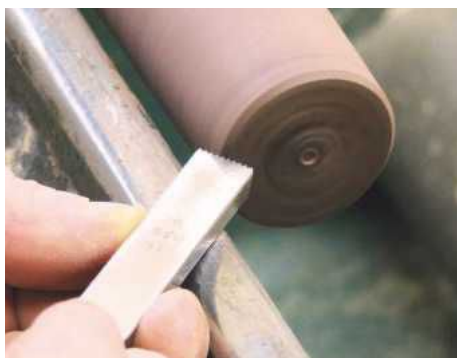
4 Practice making small circular movements on the toolrest
