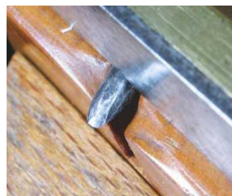
25 The nicker is for cutting across the grain
