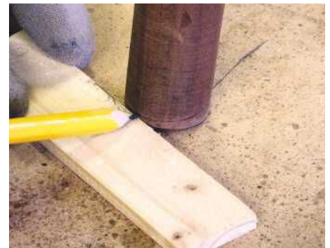
24 I got the chair level and used a piece of waste to mark where the legs needed to be trimmed
