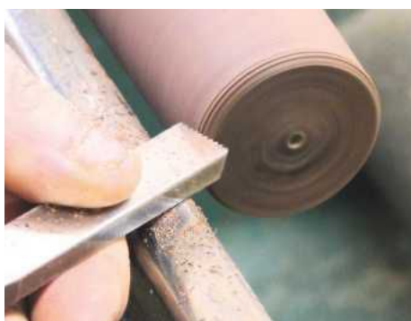
5 Make the first cut on the chamfered part of the workpiece
