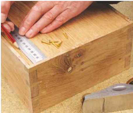
25 The back panel is held in place with No.4 brass countersunk screws. You can then mark out and drill clearance holes
