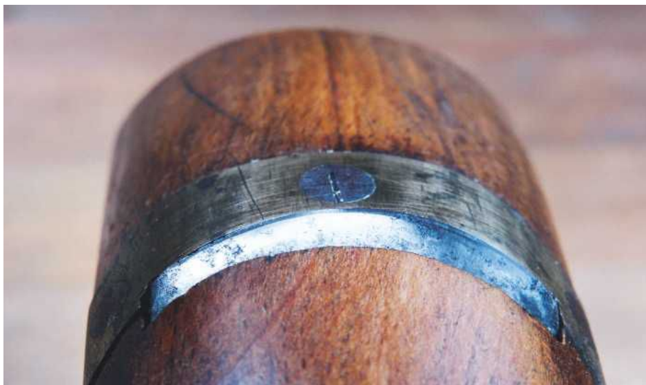
14 The radiused blade and brass wear plate
