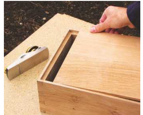
24 Check the back fits into the rebate. It should not be too tight, to allow for possible wood movement
