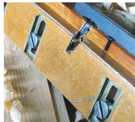
24 The fence adjusts the rebate's width
