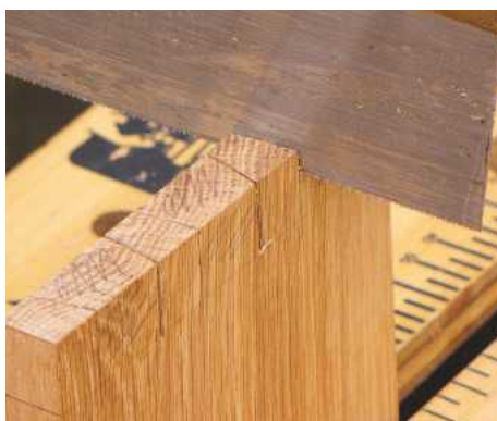
14 Continue to mark the pin lines around the ends using a square. Cut these neatly, keeping the saw vertical during this process
