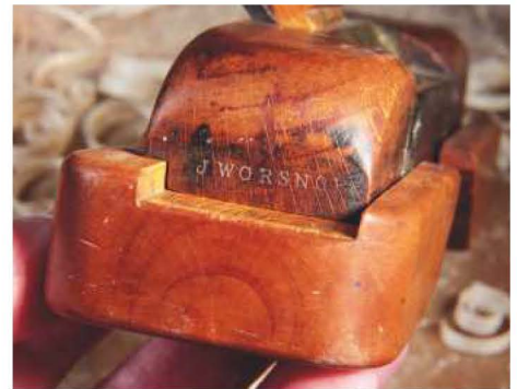
7 The end-grain of the guides runs perpendicular to the stock's
