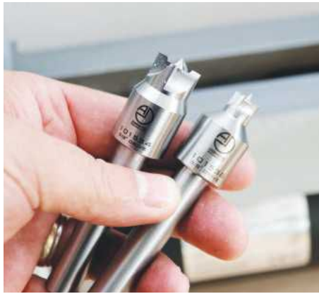
A range of drive centres are also available but require different collets to use them
