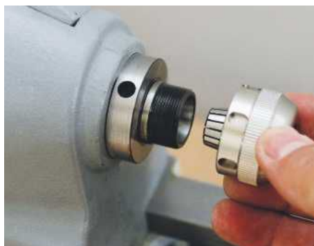
You screw the chuck directly to the headstock; there is no Morse taper at this end
