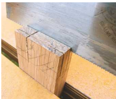
32 Haunched stub tenons are used for the frame. Saw tenon cheeks first, followed by the haunch
