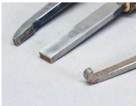
1 You will need a matching pair of chasers to cut screw threads
