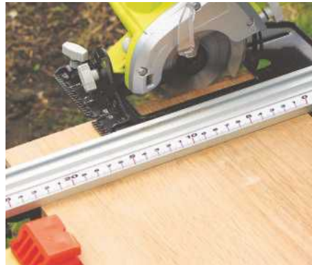
23 Plane the panel's long edges parallel and check for width. Saw to length and trim with a block plane if necessary
