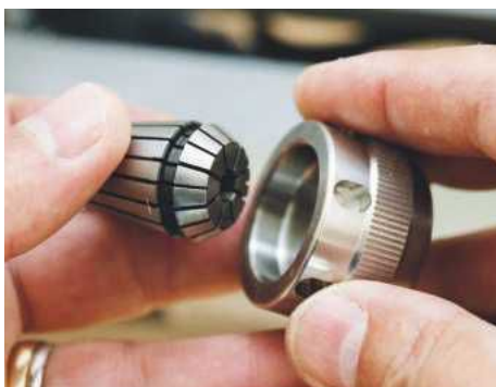
The lathe uses high quality collets to hold the various drive centres
