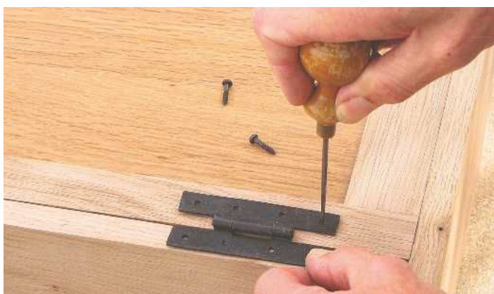
40 Hinges are easy to fit as they're simply surface mounted. Mark the screw centres with a bradawl and drill
