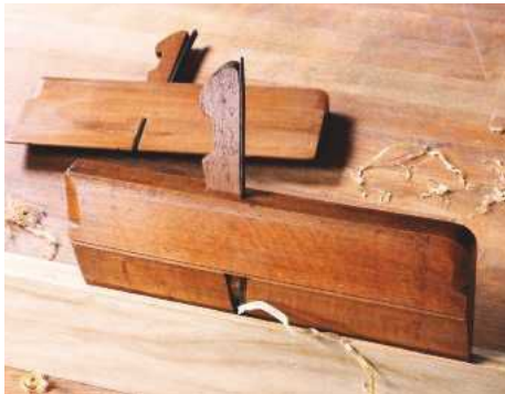
18 Side rebate planes work in grooves and dados
