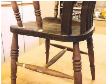
23 The gap filling, foaming adhesive had hardened and was then ready to be cleaned off
