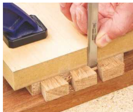
12 Cramp a square block along the shoulder line as a vertical support for the chisel. Trim back to the shoulders
