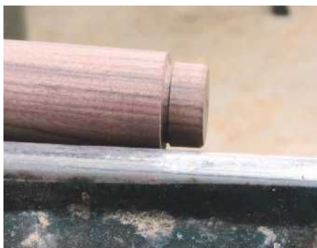
8 Male threads are normally cut on a tenon. Note the relief groove...
