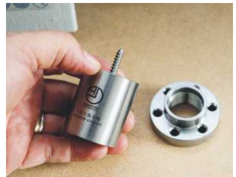
There is a small faceplate and a screw chuck that fit to the threaded spindle
