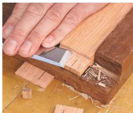
33 Carefully saw the tenon shoulders and tidy up the cheeks by paring with a wide chisel held horizontally
