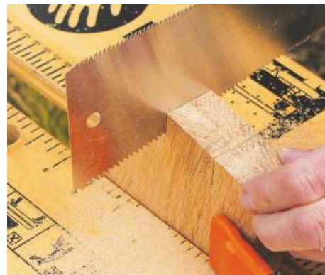
9 Cramp the sides together and saw each tail in turn, cutting carefully on the waste side of the line
