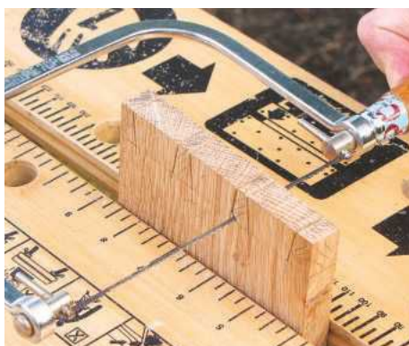
10 Remove most of the waste between the tails with a coping saw, keeping the blade completely level
