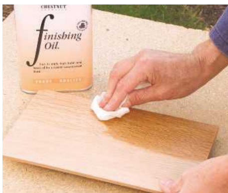
35 Sand the panel and apply oil to both sides before assembling the door. Wipe off the excess oil after a few minutes
