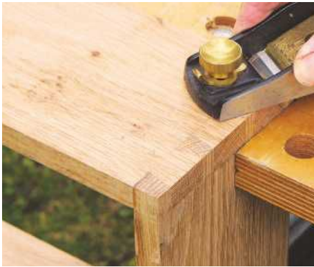
19 Carefully trim the joints flush with a finely-set block plane, working at an angle across the ends
