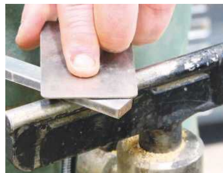
3 Sharpen the chasers by rubbing a diamond file across the top surface
