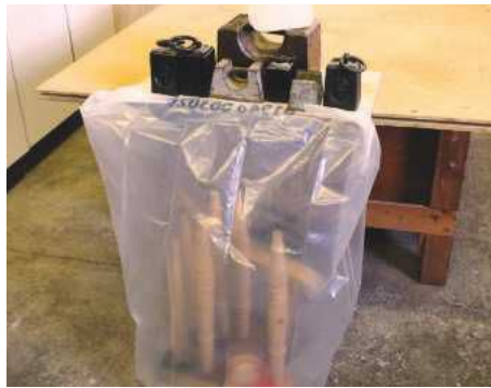
20 All the new components were sealed in a bag with some ammonia
