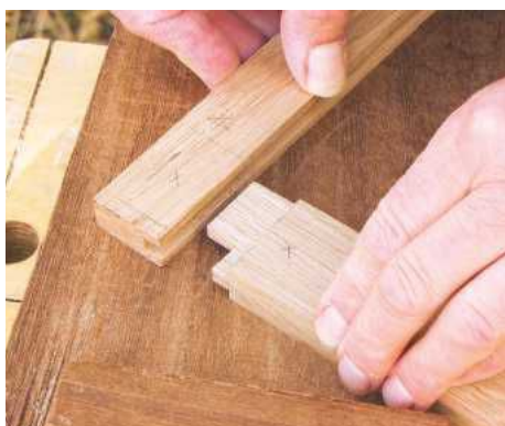
34 Check each corner joint fits together snugly. The haunch should fit neatly into the routed groove
