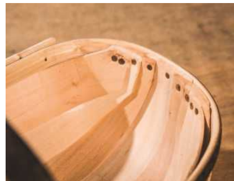
24 Copper tacks secure the boards
