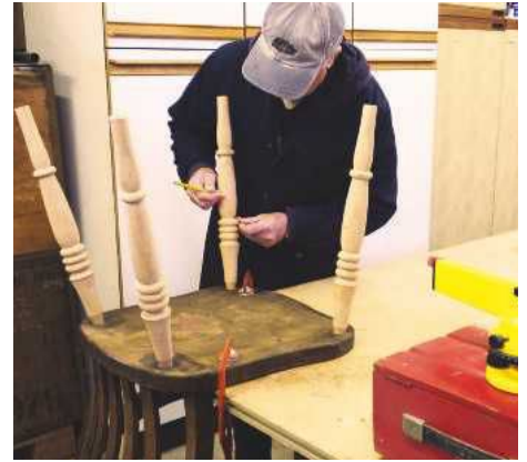
14 Using a laser to mark the stretcher sockets on each leg
