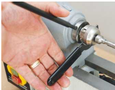
A tommy bar and pin spanner are used to tighten the collets to the drives
