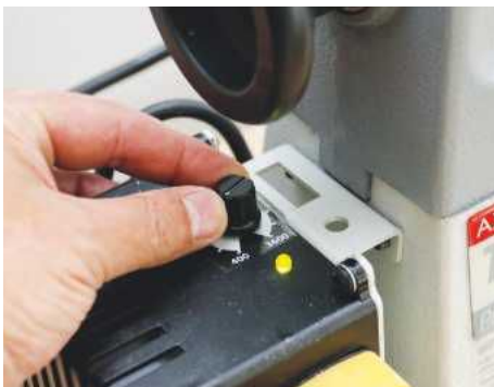
The variable-speed runs from 400-3,600rpm and works very smoothly throughout
