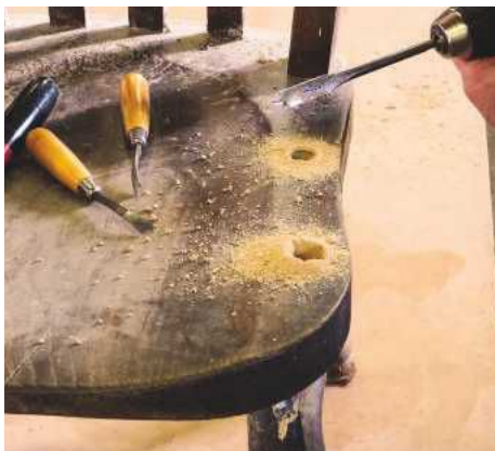
5 All the joint sockets required the broken off, wormy stuff to be removed and the loose stuff cleaned out
