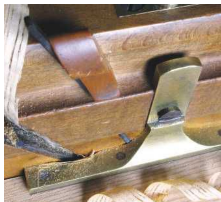
23 Depth stop, nicker and its boxwood wedge
