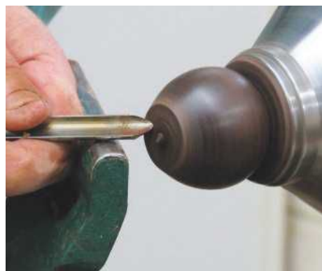
23 ... and cut a male thread on scrap wood to screw the base onto to complete the bottom
