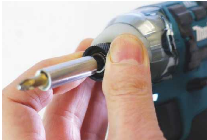
The pull-down collar releases the driver bit; note effectiveness of onboard LED worklamp
