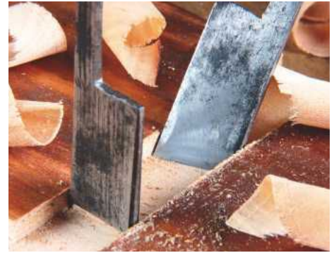
17 Showing how the double-spurred nicker precedes the blade
