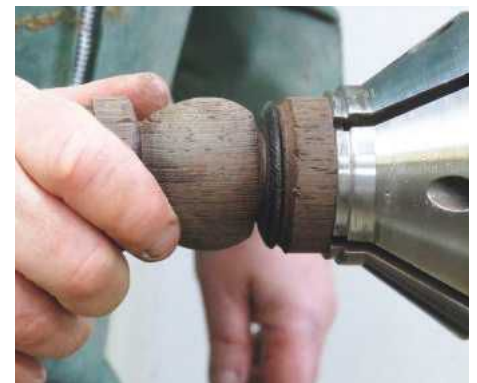
18 Initially, the threads were a little too tight
