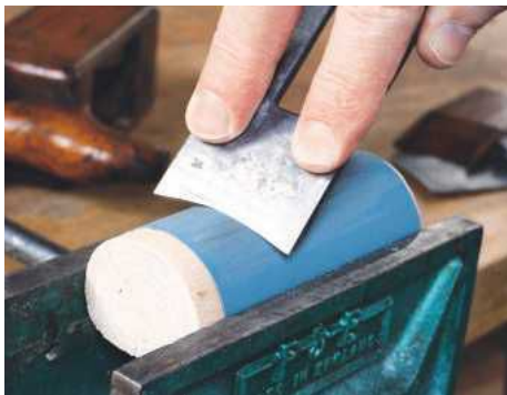
11 Sharpening with abrasive paper on a former
