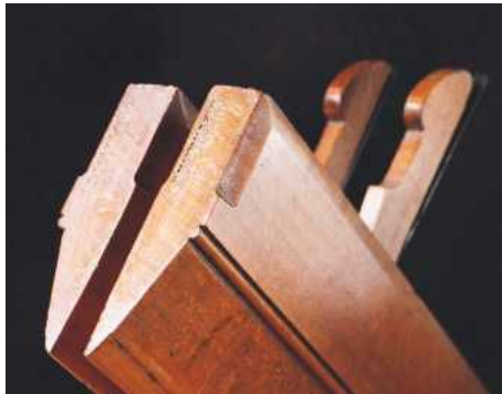
19 Left and right planes are mirror images
