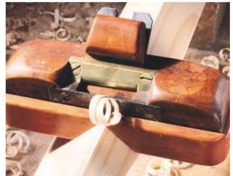
5 The chamfer plane straddles the arris
