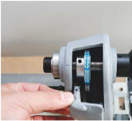
The lathe is driven by a single belt, which is accessed via a hinged flap
