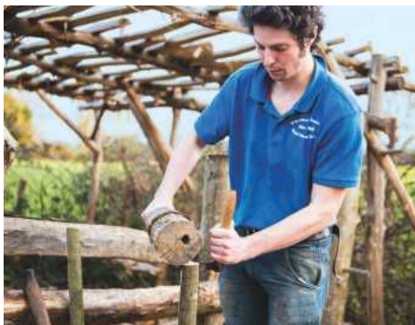
9 The craftsman uses a cleaving axe and wooden maul to split the chestnut
