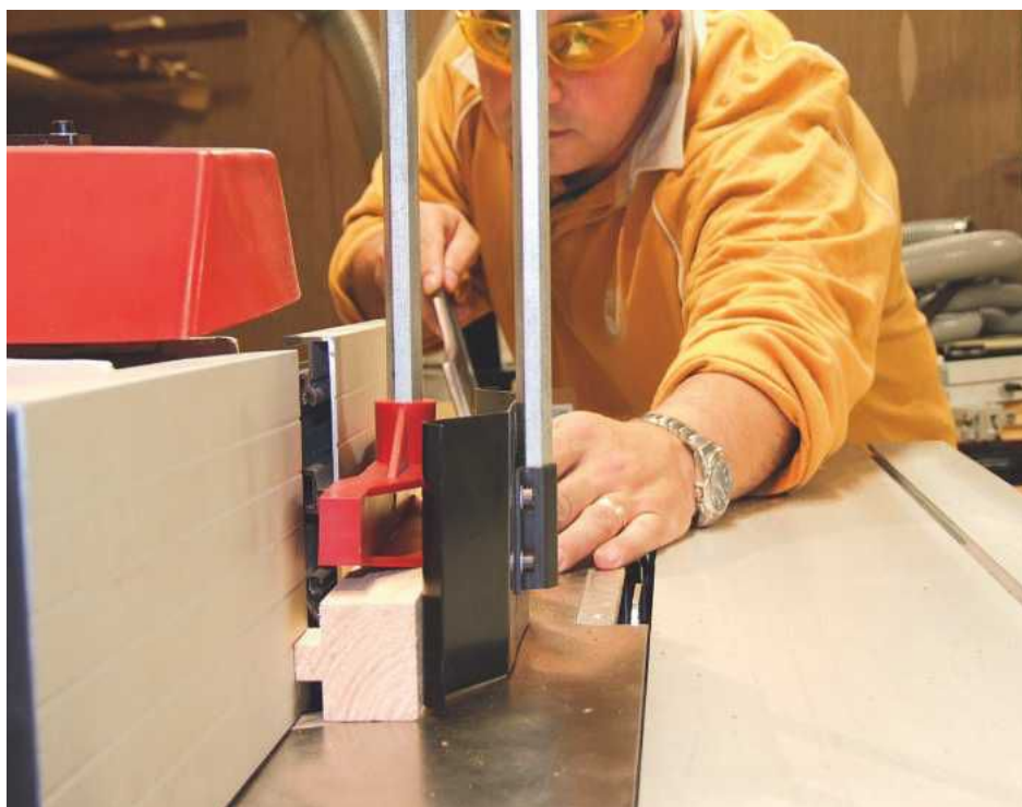
I like the spindle moulder on the Axminster AW4 Universal, but would prefer wooden facings to the alloy one supplied – an easy modification
