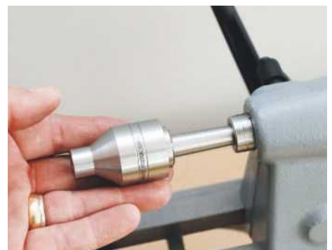
The tailstock has a standard Morse taper fit for live centres and such like
