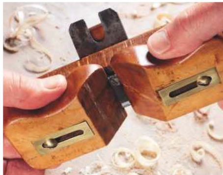
6 Hollows for thumbs in the boxwood guides
