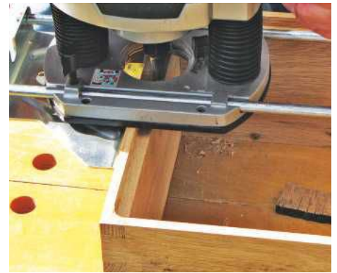
21 Rout a rebate around the rear edges for the back. You'll find this is easier to do before you start to glue up the cabinet...
