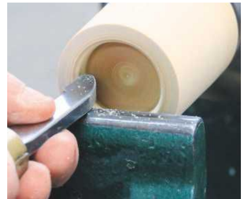
12 ... then swing the handle to cut down the side wall of the recess
