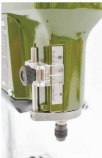
The calibrated depth stop, which remains positive when set
