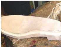
17 The groove or rebate, which has been cut with the gripper knife
