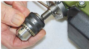
It is easy to screw the ROHM chuck to the threaded drill shank in place of the collet holder
