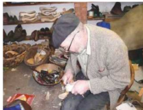
18 Cleaning out the groove with a Stanley knife
