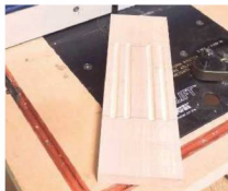
3 Reversing the timber between each pass and moving the fence back between the second and third got me two pairs of stopped flutes
