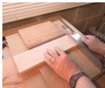
1 The end of the blank was squared up and smoothed on the shooting board
