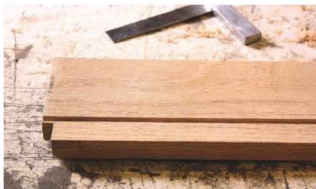
2 Top board of cabinet with groove for housing
