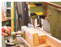
14 Mortising the stiles
