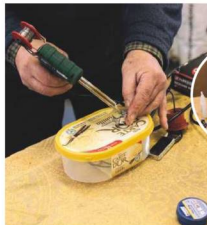
8 ... then solder the wires to the positive and negative ends of the jack plug
