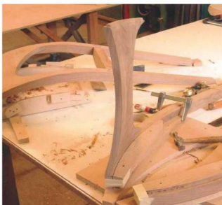
4 The legs were eventually fitted into the yokes
