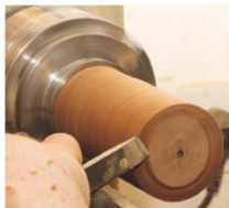
26 Using a skew chisel, turn the end square, then turn down the end to fit in the bottom
