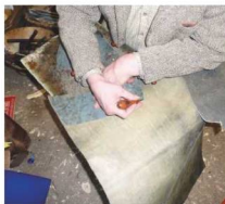
22 Marking out the leather using the templates
