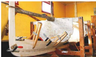
The boat is built inside a rig. Here you can see the three white templates determining the boat's profile from bow to stern
