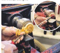
5 Turn the top, holding it on a jam chuck, then drill a 10mm hole for the jack plug
