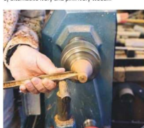
9 Turn a pair of cones to friction hold the slides; these will allow you to complete the turning and sanding
