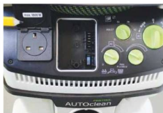
Close-up of controls; note appliance socket and centre blanking plate, which has been removed to show housing for Bluetooth receiver
