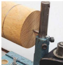
4 Ensure the cutting edge is at centre height
