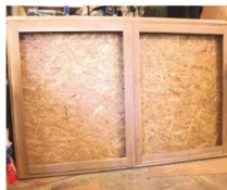
18 Glued and cleaned up, doors prior to fitting
