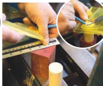
6 Another type of slide can be made using wood or acrylic. To make one, mark the centres of a piece of alternative ivory and pink ivory wood...
