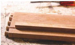
3 Cabinet base with dovetails – doorstop temporarily tried in position
