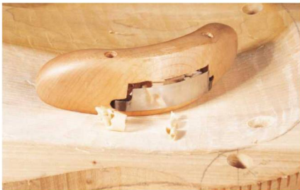
5 The travisher is a curved spokeshave, which is used for hollowing out seats
