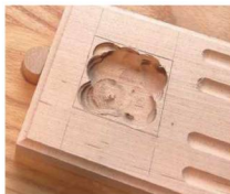
9 The roughly cut mortise just needs a bit of tidying up...
