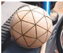
13 A ball marked out with burn lines connecting the 32 points
