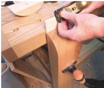
25 Finally, I worked a chamfer round the edge of the blotter's top plate
