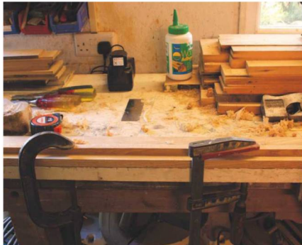
7 Doorstop being glued into position
