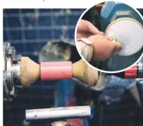
11 Sand the ends of the slides to a finish, using a sanding disc
