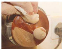
23 Turn the top around, sand, and finish off with a coat of sanding sealer
