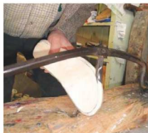
16 The gripper cuts the rebate for the leather uppers to sit in
