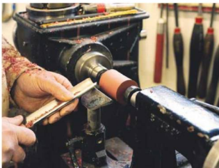
1 The first step is to turn the jack plug holder using a piece of pink ivory
