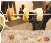
6 Polish the top and bottom with three small mops loaded with tripoli, then buff using carnauba wax
