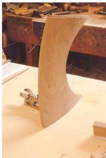
8 A finished yoke ready for fitting
