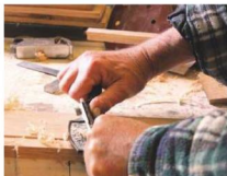
6 Cleaning up the inside of the cabinet with a scraper plane
