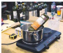
3 To remove the neck and get a clean break, you need to boil the bottle in a pan of water...
