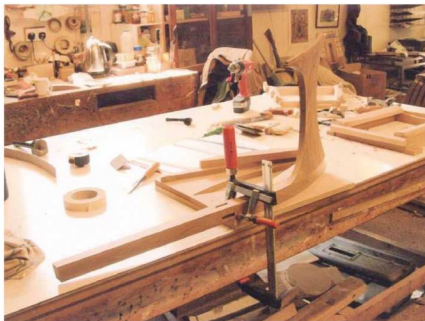
5 The shoulders were tested for true – that is, no gaps
