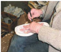
12 Drawing the line back on and preparing to cut a bevel with a blocker knife
