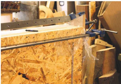
10 Gluing up frame – note cling-film to stop back being glued unintentionally
