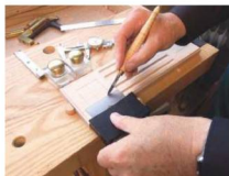
7 For the antique inkwells, I began by marking the mortises on the timber
