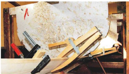
The build in the rig: boards are kept in place by wooden and metal clamps; note the piece of wood inside at the nearest metal clamp, preventing marks from the metal in the softwood; the white template is outlining the boat's profile
