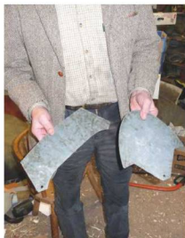
21 Different templates are used to make a particular style of clog
