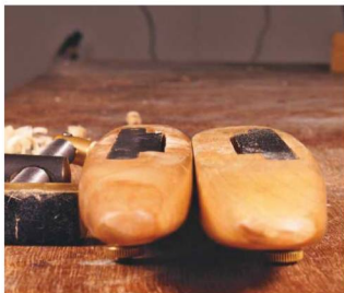
2 The angle between the blade and the nose is greater for wet wood (left), but almost nonexistent for dry wood (right)
