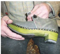
31 Button attaching strap – rubber heel and sole are nailed to the wood
