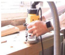
8 I then took out most of the waste by repeated overlapping plunges with the router, used freehand
