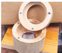
7 Prepare a simple cage chuck to hold the ball
