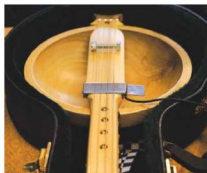
10 Attach the pick up using self-adhesive hook-and-loop-backed material; this allows the pick up to be used on several guitars
