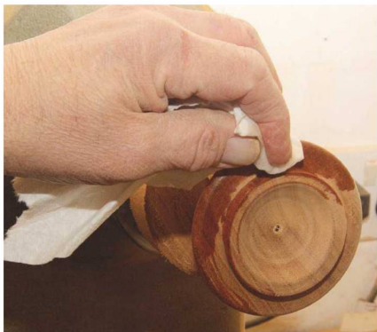
22 Apply a coat of sanding sealer to the top of the pomander
