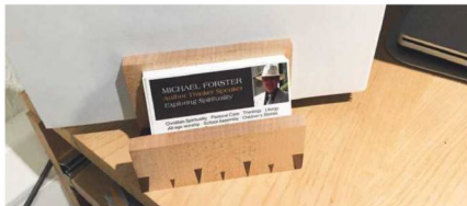
12 The houndstooth dovetail is a great decorative feature – and for causing dropped jaws at craft fairs! However...
