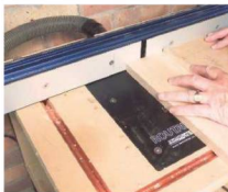
4 I then reset the fence to cut the edge flutes. Always complete the cross-grain cuts first so that any breakout will be in the waste
