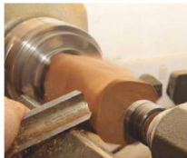
24 Finally, take the smaller piece, mount it between centres, and turn it to the round
