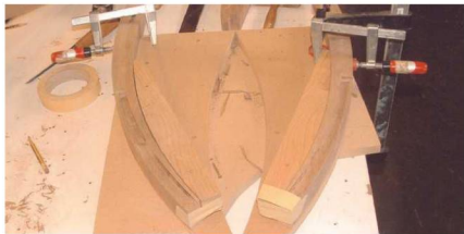
2 I had to trench the legs so that they would take the yoke
