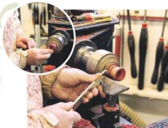
4 Turn the shape on the outside to that of a small top hat and sand through the grits to 600
