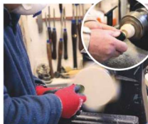
5 You can then sand the bottom, outside and inside, with water and abrasive to smooth the sharp edges
