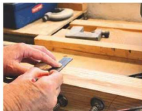
13 Marking out door mortises with the stiles clamped together
