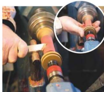
10 Turn, sand and finish with abrasive to 600 grit, then burnish with shavings
