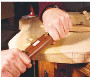
3 Newcomers to the spokeshave tend to grip the handles in both fists, making fine cuts nigh on impossible...
