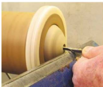
11 Undercut the hole slightly, but don't enlarge the opening
