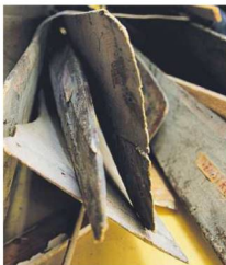
The boards from the old Nordlandsbåt. During the dismembering process, each board was identified and marked
