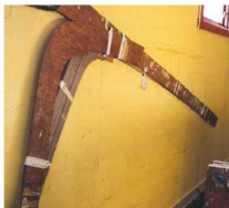
On the wall hang the bow and stern templates
