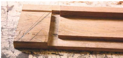
4 Cabinet side showing stopped housing and rebate for OSB back
