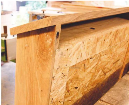
11 Rear view with roof fitted – note pocket screws and holes for vents
