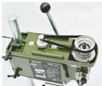
The top casing is quickly removed to reveal the flat belt and aluminium pulleys
