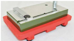
The table also has two holes, which allows the machine to be screwed to a bench or base
