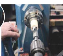
8 Drill both pieces of material from each end to a diameter of 19mm
