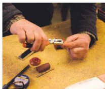
7 Trim the two wires and tin the bare ends with a soldering iron...
