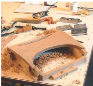
3 Spokeshaving the yokes was a long task. Note the 4mm lath (or fillet) on the inside semicircular edge, which covers the end-grain
