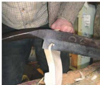
13 Cutting the bevel using the blocker knife
