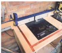
2 To cut the flutes I clamped end-stops of scrap to the router table fence
