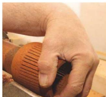
27 Check to see if it goes into the hole – you're looking for a tight fit here
