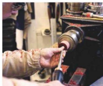
3 Next, drill a hole through the material to a depth of 10mm diameter, then hollow the bottom section of the jack plug holder using a 10mm bowl gouge with a swept-back grind
