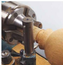
6 Part off, leaving a stub big enough to complete the curve of the ball
