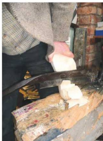
8 Blocking out the underside
