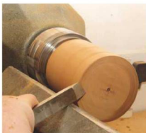
17 True up the piece, using a skew chisel, then shape the end so that it will be a nice loose fit in the bottom of the pomander
