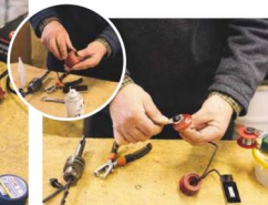
9 Tighten the locking nut on the jack plug and glue the two pieces together – I use Chestnut Products' thick CA adhesive
