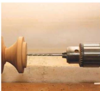
20 Here I am drilling a hole through the top of the pomander
