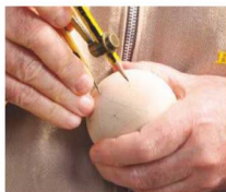
9 Draw circles carefully and keep checking that the compass setting hasn't changed
