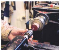
2 Take a piece of material measuring 50mm long x 45mm square and turn it to the round
