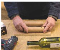
1 I made a jig to cut wine bottle tops, using a standard glass cutter
