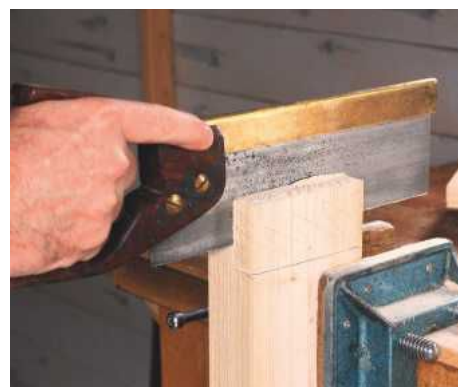
11 Ripping a halved 'T' joint with the Double Century tenon saw
