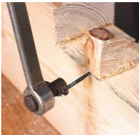
20 Removing an inconvenient knot
