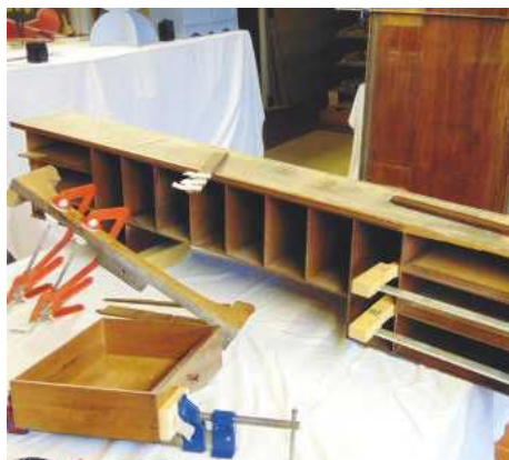
12 Step-by-step, pieces are re-fixed and loose joints glued up
