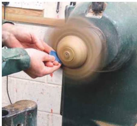
14 Hand sand the solid parts...
