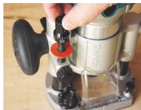
There are comprehensive fine adjustments on the plunge base
