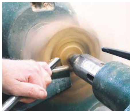
5 Use a pull cut to flatten the bottom...
