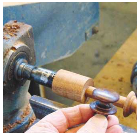
22 To start, two knobs per section are placed between centres
