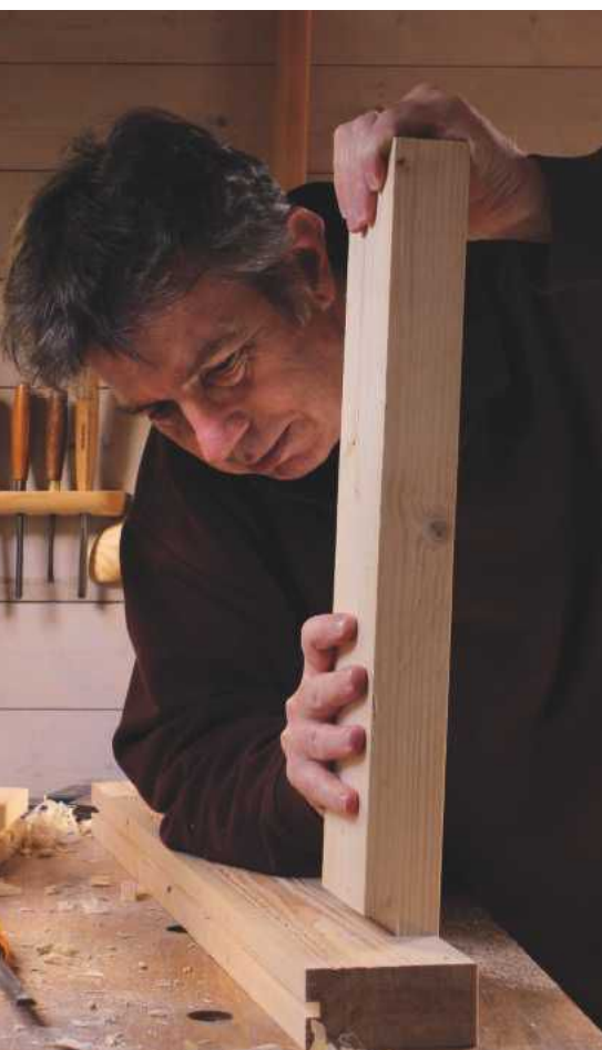
23 Test fitting the legs in their notches
