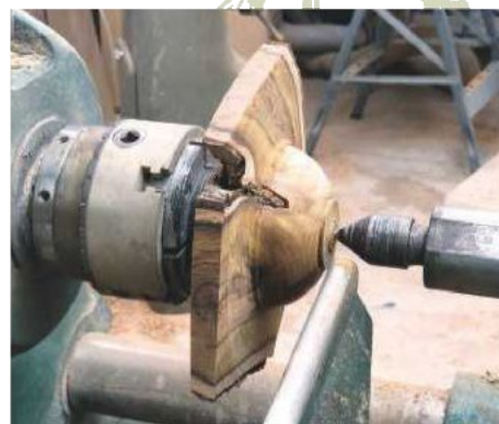
12 The final shape of the underside of the bowl
