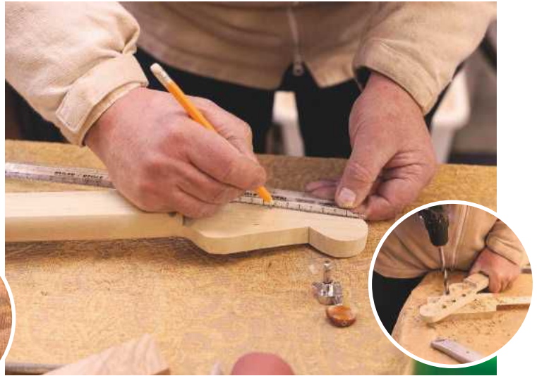
15 You can then mark and drill the machine heads. Most are 10mm, but check the size that you buy. I get most of my guitar hardware components on Amazon
