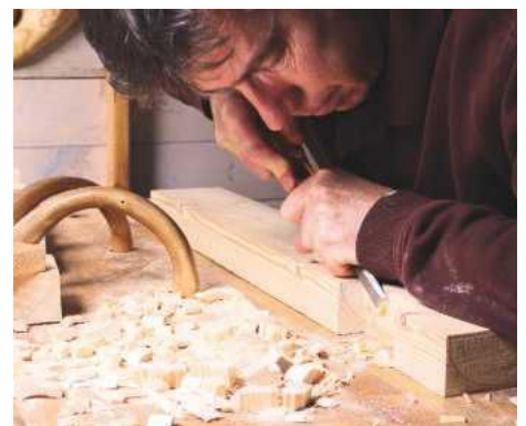
19 Chiselling out the waste
