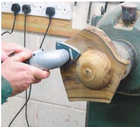
16 Sand the underside of the wings with a delta sander with the lathe switched off
