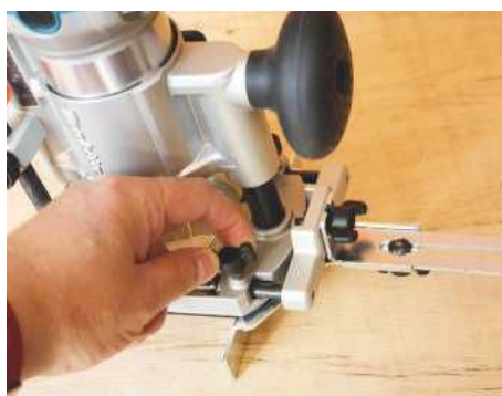
It also comes with an adaptor that allows it to fit to the plunge base
