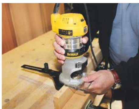
Fitted with the fence and steadying the base keeps it stable for edge mortising or grooving
