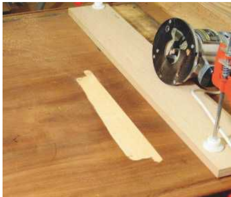
18 First cuts into the desk top for the skiver
