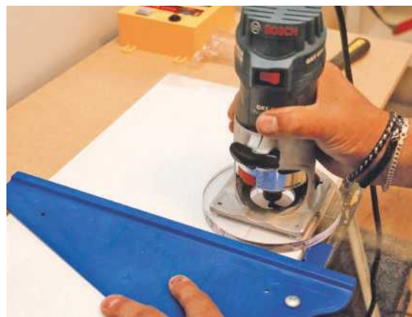
The round base takes guide bushes and is useful against straight edges
