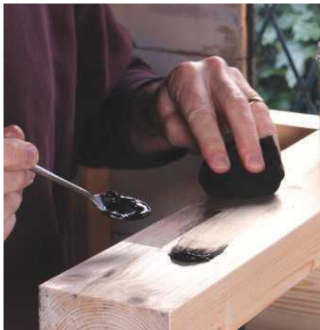
32 Rubbing in the black wax-oil finish
