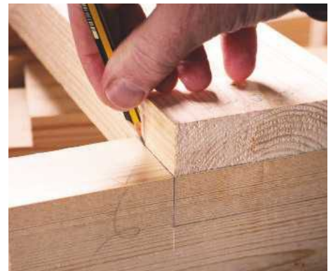
17 Marking out for the leg's 'T' joint
