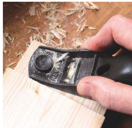
22 Fetting a surface with the Record 102
