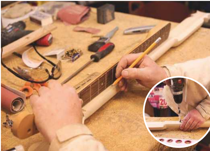
16 I now mark the fret marks and drill the holes to house 10mm upholstery studs, as the Blues bowl shown here is a fretless instrument. If you prefer, you could use a branding iron as shown in step 9
