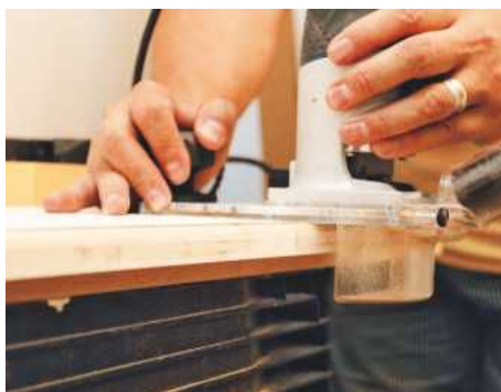
Dust control is excellent with the edge dust collector kit fitted
