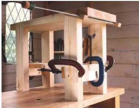
29 In cramps for the last stage of gluing
