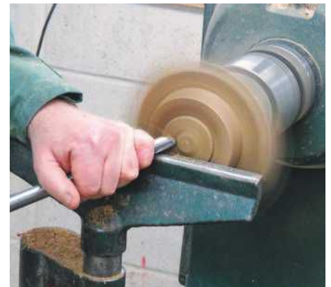
18 Remove the temporary spigot with a pull cut
