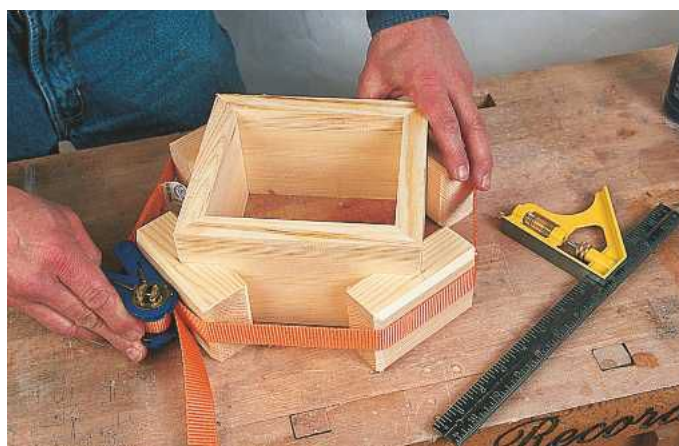
Strap cramps and corner blocks are the best way to cramp up a mitred box
