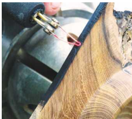
25 I used a pyrography machine to burn the edges
