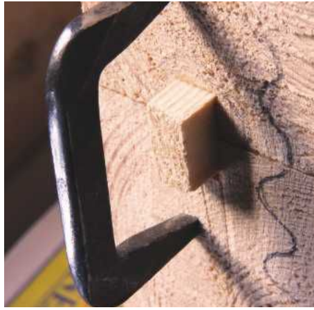
27 The dog's tapered legs pinch the joint
