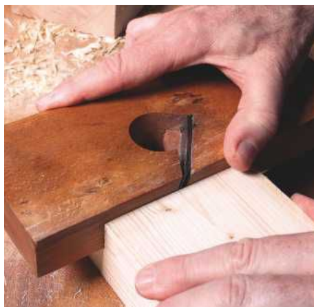
21 Straightening a shoulder with the rabbet plane
