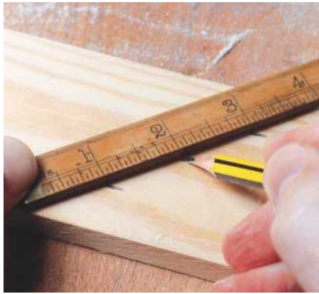
14 Dividing four equal widths for loose tongues
