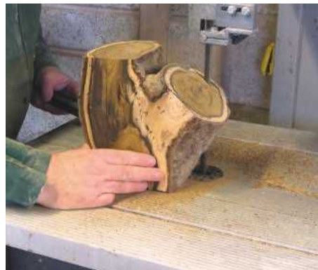
2 Cut a small slice from both sides to create a flat
