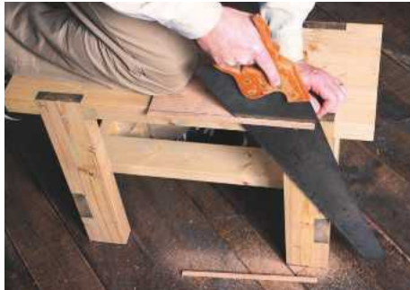
1 Vertical legs permit ripping close to the long edge
