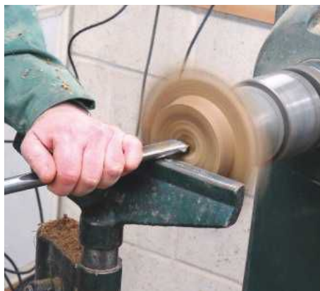
20 Swing the handle towards you and rotate the flute anti-clockwise
