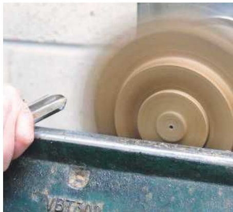
17 Another shot of the push cut, this time to reduce the thickness of the wings
