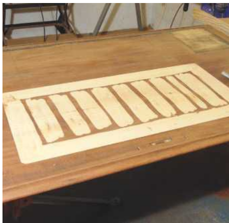
20 The vast majority of waste is cut out of the skiver recess leaving areas of 'land' that are trimmed out by hand
