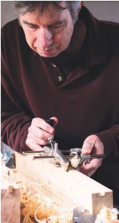
13 Keeping the fence up to the work
