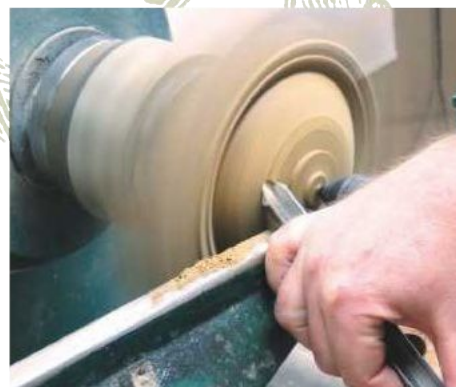
9 Shape the underside of the bowl using a push cut...
