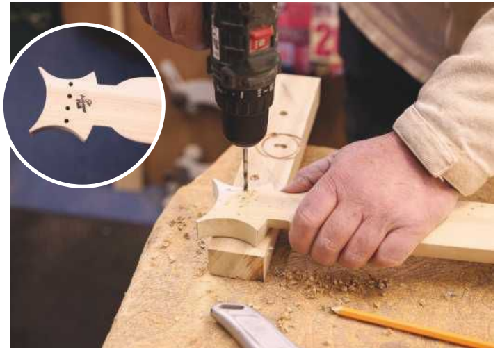
17 Drill the string holes to 3mm diameter. I use pop rivet sleeves to protect the wood from the strings and allow the ball of the string to cushion against the rivet. The strings are 12mm apart
