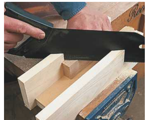
Make your own deep-sided mitre box to control the saw when sawing mitres by hand
