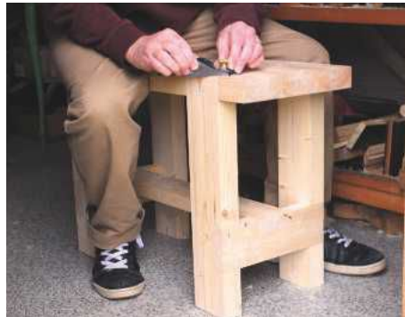
30 Seated for planing end-grain of the legs
