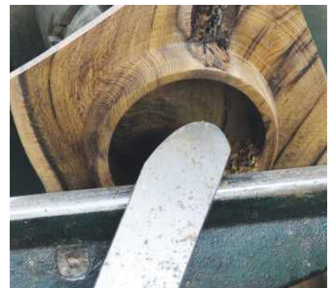
21 My French curve round-nosed scraper
