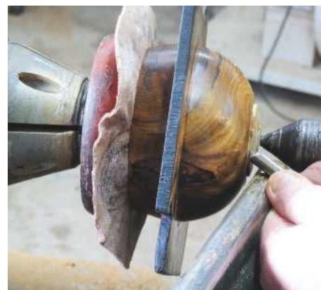
27 Reverse chuck the bowl onto a dolly to remove the chucking spigot
