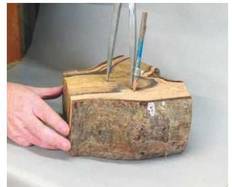
3 A pair of compasses shows where the bowl part will be
