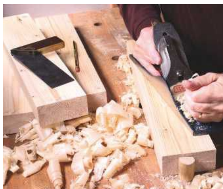
10 Planing cupped timber flat for the legs
