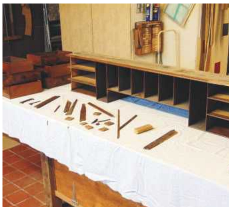
11 Repairs start by sorting out the bits that had broken off the top drawer and file unit
