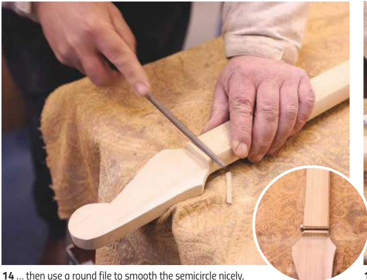
14 ... then use a round file to smooth the semicircle nicely, which houses a 6mm bolt
