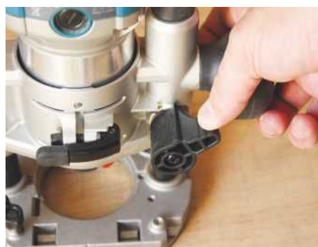
The stubby plunge lever needs to be pushed to lock it
