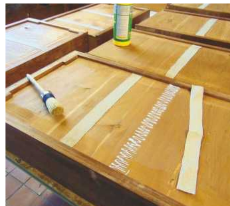
13 An easy way to stop cracked drawer bottoms rattling is to glue strips of tough fabric over the gaps
