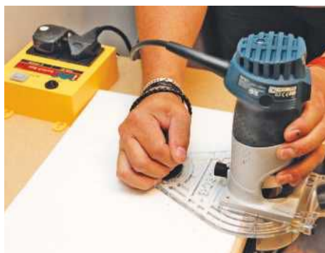
There's excellent support for the router with the tear-drop base fitted
