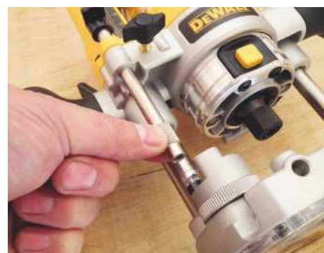
You can make micro adjustments to the plunge post with this fine adjuster
