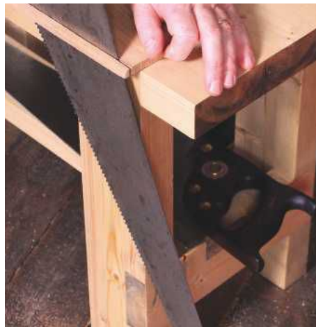
33 A stable platform for sawing away from the workshop
