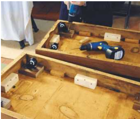
17 Originally there were only two castors on each stack of drawers, but four is much better and gives more stability
