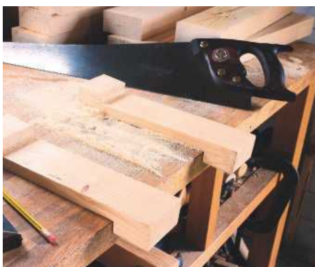
9 Bench hooks are invaluable aids to sawing
