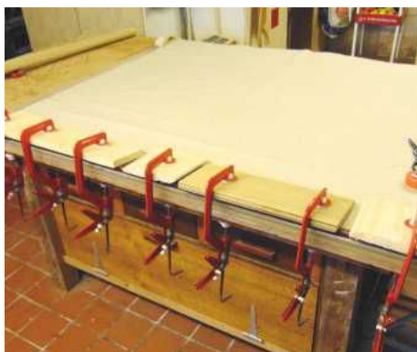
2 The first tambour strip is glued onto the edge of the new backing cloth
