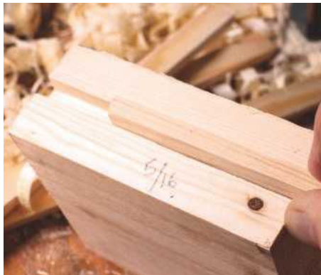
16 Gauging the fit of a loose tongue
