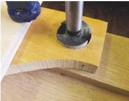
25 Drilling the centre hole
