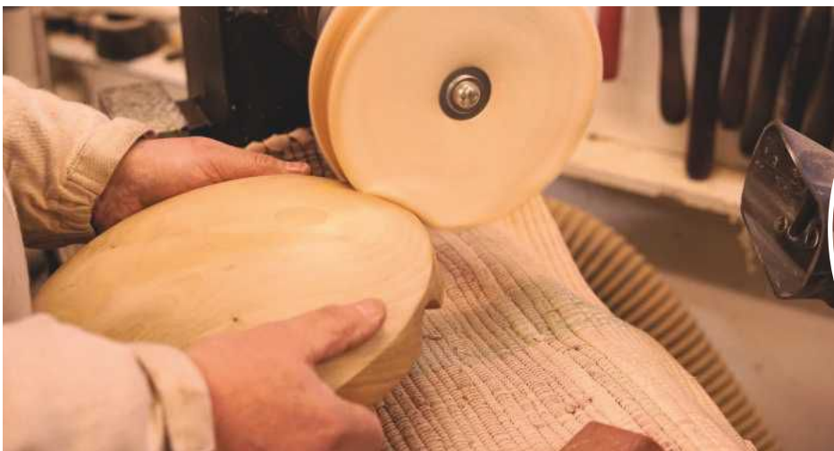
18 Now it's time to apply a finish to the Blues bowl and here we have a couple of options. For the Blues bowl described in this project, I have used the Beall buffing system, but you could also use the Chestnut buffing system and get the same results. It's a three wax process: first, a coat of Tripoli is applied, then white diamond and finally Carnauba wax. I find this gives a silky smooth finish and is quick to apply and process. I have used this system for a number of years and have always applied sanding sealer before the first coat of Tripoli. Having spoken to Peter Hemsley from The ToolPost, who stocks the Beall system, he suggested not using the sanding sealer as this gives a better finish. I tried it and agree, as the sanding sealer seems to dull the final finish, but try both ways and decide. Note: I always place a piece of carpet or soft material on the bed of the lathe as it can sometimes grab and pull the material down. If it happens, this safety precaution can help prevent the material getting marked or bruised. The alternative method is to spray the Blues bowl using Chestnut lacquers in green for satin, blue for gloss, and orange for melamine, which is the most hard-wearing. My latest Blues bowl banjos have been sprayed with a waterborne lacquer, which is totally odourless and safe. However, I always wear a solvent filter mask whenever I lacquer, no matter which one I use
