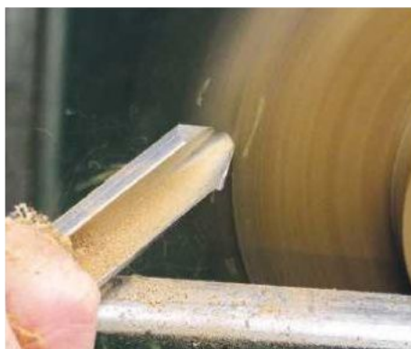
11 Here's a close-up of the previous cut showing where the shaving is coming off
