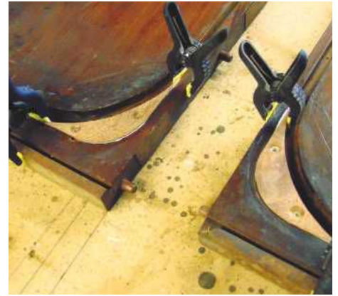
16 The tambour track trench had been modified, so I decided that it ought to be sorted properly with a new set of inserts
