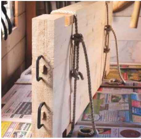
26 Cramping glued joints with joiners' dogs
