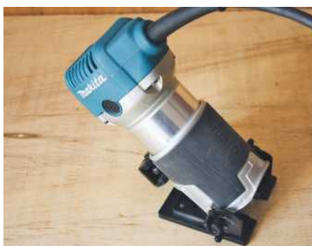
Handily, you can use the tilt base across a range of different angles
