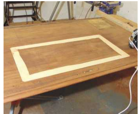
19 The outline of the recess is cut leaving the corners to be trimmed by hand later on
