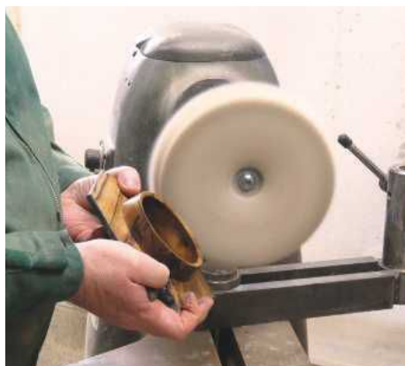
28 I buffed my piece using the Beall buffing system
