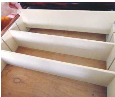
24 Final touches are some slip-in divisions for three of the drawers
