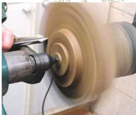
8 Use a push cut to lower the wings
