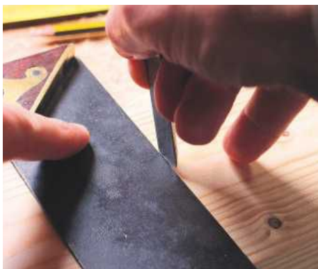
6 Marking all round with try-square and chisel...
