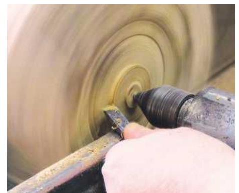
6 ... and a skew chisel to cut the dovetail spigot
