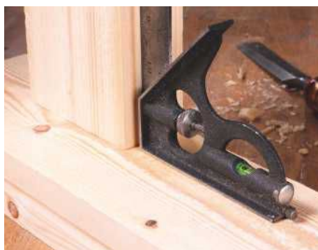
24 Checking perpendicular with the combination square
