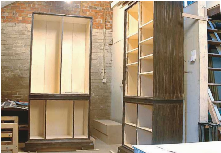
1 The two cabinets part-way through construction. You can see the different uses of the interiors – Number One on the left is the workstation cabinet, while Number Two provides lots of filing and storage space
