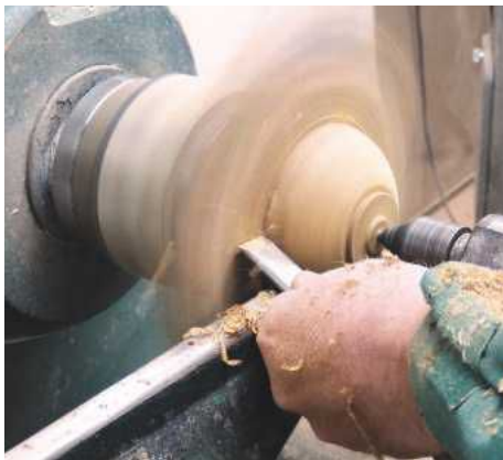
13 Use a skew chisel to scrape the wings
