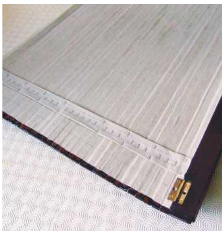
8 Once all the tambour strips are glued on, a couple of extra straps of backing are stapled in place
