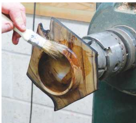
26 Apply a coat of sanding sealer
