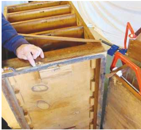
15 When old knocks and losses have occurred, new pieces are grafted on
