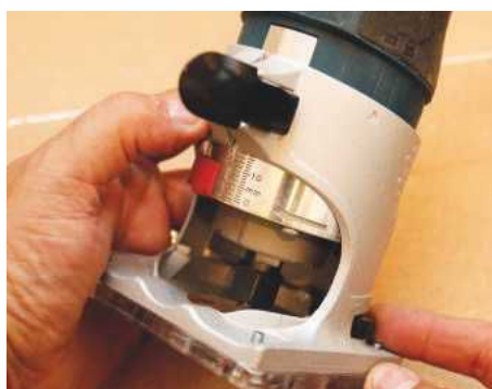
A fine adjustment wheel on the tilt and fixed-base read against the etched scale
