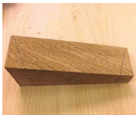
13 East planed and ready to be cut to length
