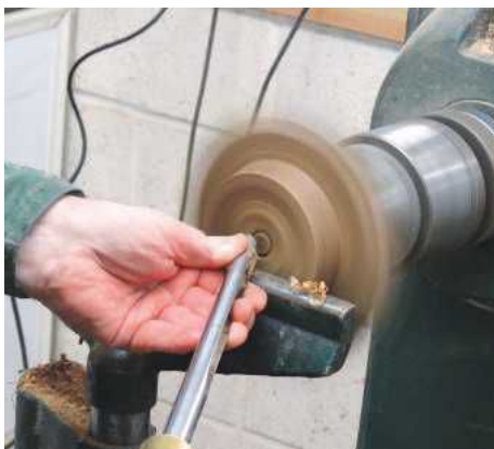
19 Start to hollow the bowl with the tool handle well over the bed bars
