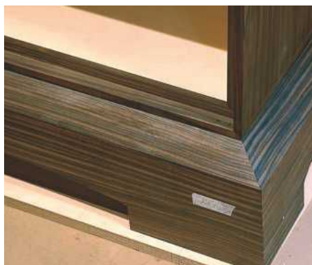
3 Broad-bevelled plinth being marked up
