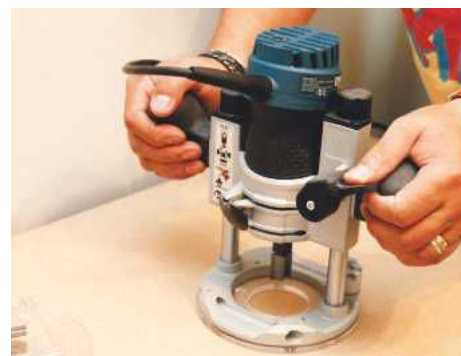
The plunge base lever action is top drawer; very easy to access and operate
