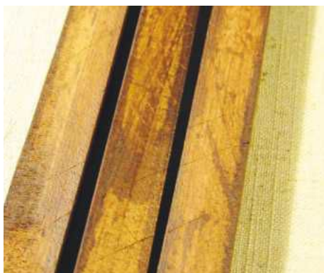
5 Each tambour strip is cross-hatched on the back to aid adhesion
