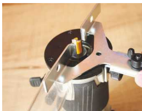
The simple pressed steel fence quickly fits to the fixed-base
