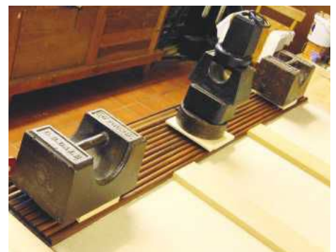
7 Nine strips and that's the width of the weights I'm using to hold them in place. A couple of gash pieces of stock are used to tighten the strips together
