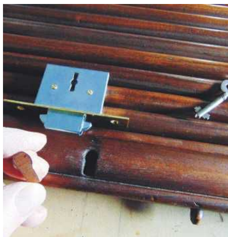
9 This little plug is 'fettled' to fit the old key hole
