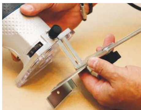
The supplied fence only fits to the fixed-base but is easy to adjust
