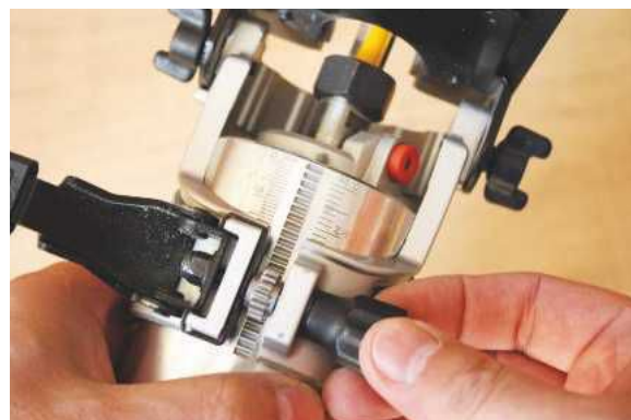
A rack and pinion allows easy adjustment, but there's no fine-tuning
