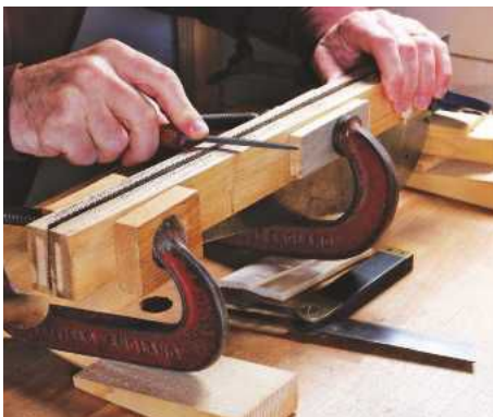
5 Using a sliding bevel as a guide to the angle of the file
