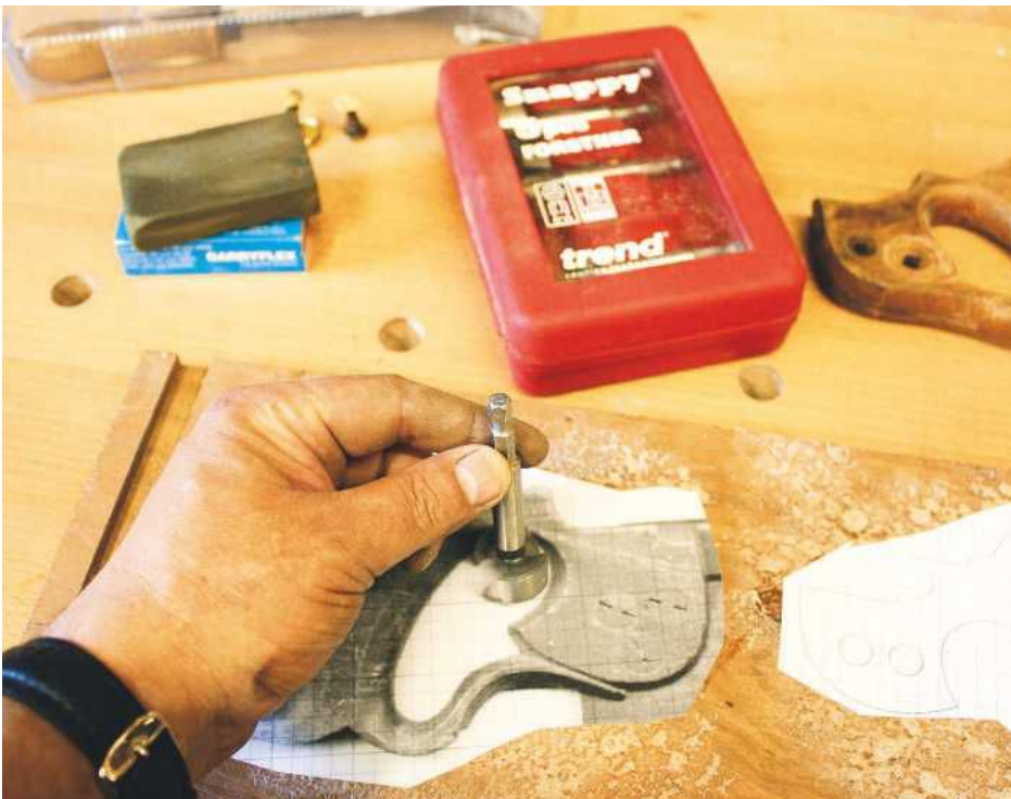
2 Use of a drill and Forstner bits produces the cleanest holes...
