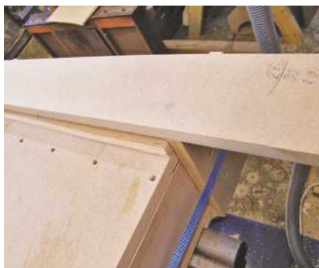
14 The MDF guide is level with the edge of the upright timbers
