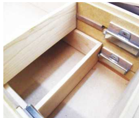
21 Fit the spring-loaded drawer openers before the top is glued in place
