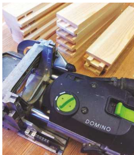
14 All the component parts Dominoed and ready for gluing
