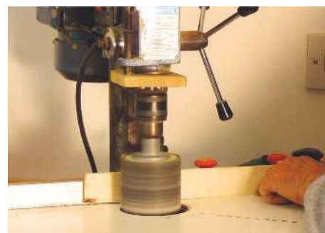
8 With a little ingenuity, I was able to turn a drum sander into a thicknesser...
