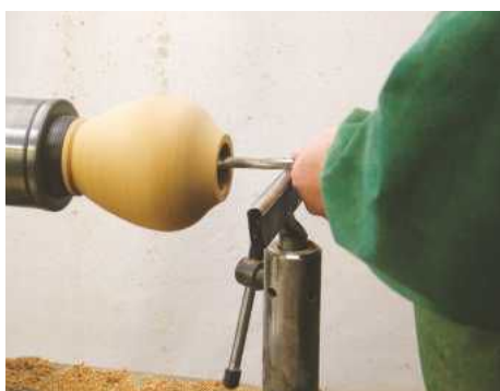
16 ... and clean up the inside as necessary
