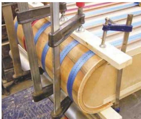
10 Note the timbers cramped to press the plywood flat
