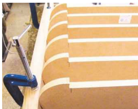
3 Cut the formers as shown in the photo
