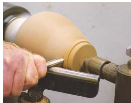
21 Complete the bottom of the vase...
