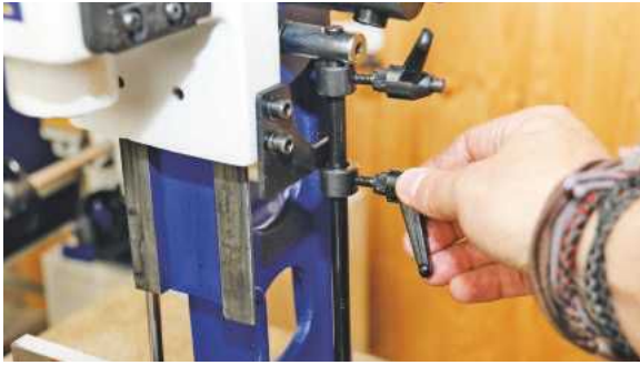
Clamps are used to restrict plunge for stopped mortises or haunches
