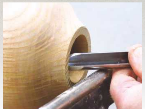
9 When the hole is large enough, use a swept-back gouge on its side
