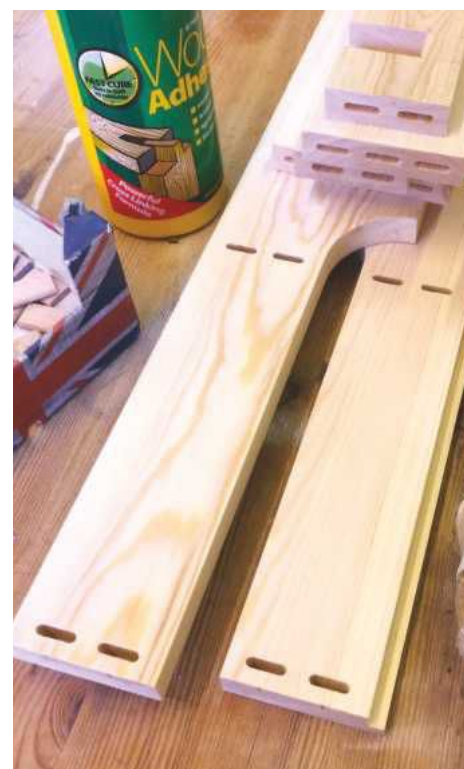
8 After a trial assembly, the carcass is ready for the glue-up
