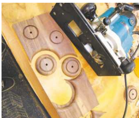
25 The N-Compass jig is made for this part of the job
