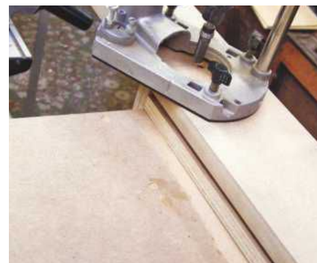
15 Use a bearing-guided trimmer to level the edge
