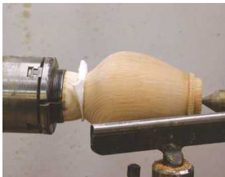
20 Mount the vase onto the dome and use the tailstock to hold it in place
