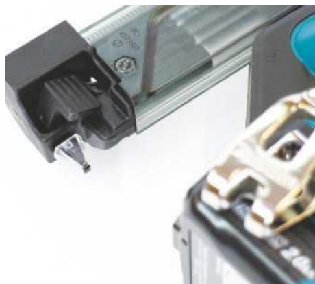
The spare nailer tip, standing by
