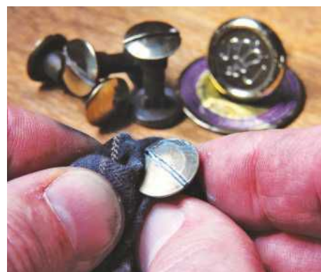
12 Cleaning the saw nuts and Double Century insignia
