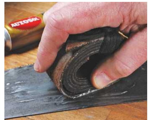
7 Polishing the blade with Autosol and a rolled leather strap
