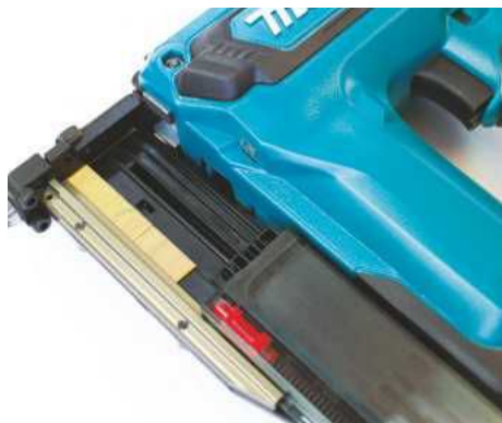
Magazine open, and showing red indicator
