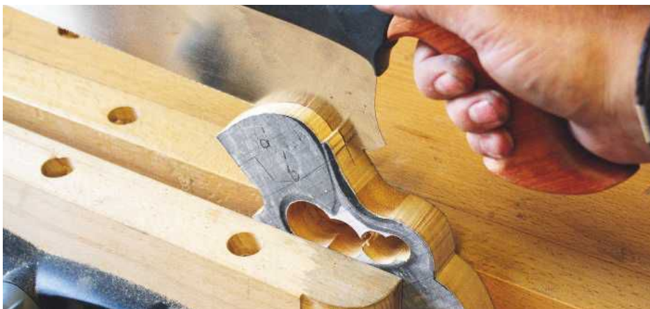
6 Cut the saw using another fine saw
