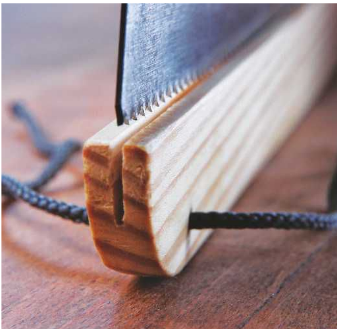
32 Saw teeth are protected by the new edge guard
