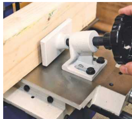
The angled clamp holds the work very firmly to the fence and table
