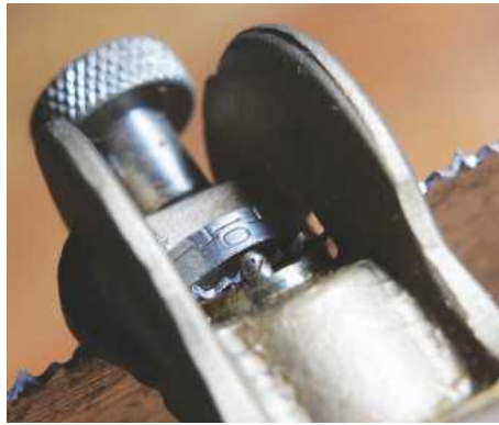
15 Close-up on the plunger and anvil set at 10
