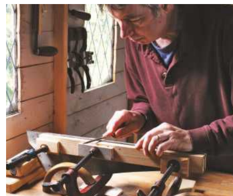
4 The saw clamp of oak battens and G-cramps anchored by crook holdfasts
