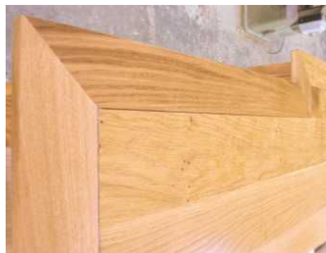
I incorporated a 3mm groove into the cabinet's top, bordered by a mitred frame
