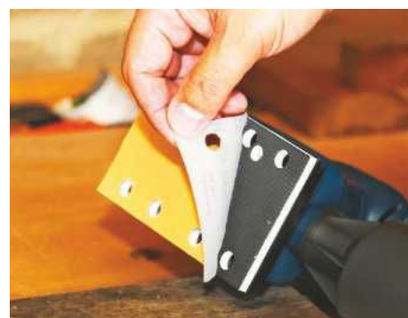
Hook-and-loop bases are common across all three for more efficient sanding
