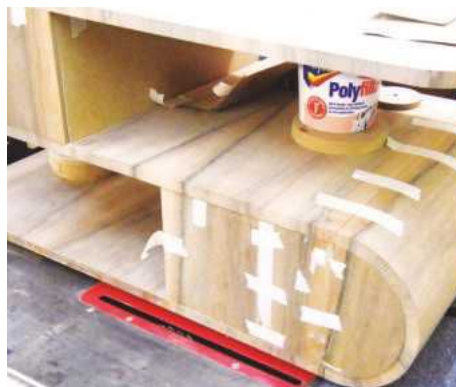
20 Several dry runs later to make sure everything fits together
