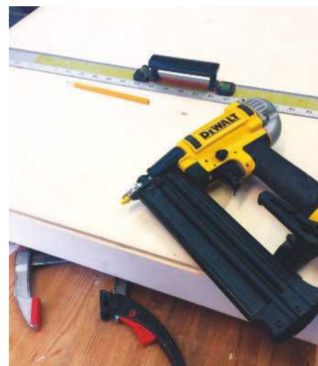
11 The back is pinned on; note 5mm gap at bottom (grrr!)
