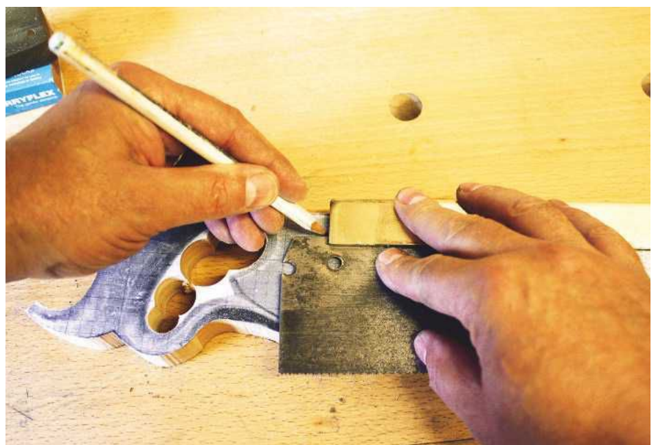
5 Draw the outline of the blade, the screw holes and where the spine will sit
