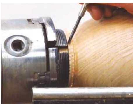
4 Avoid a gap here; it will weaken the hold
