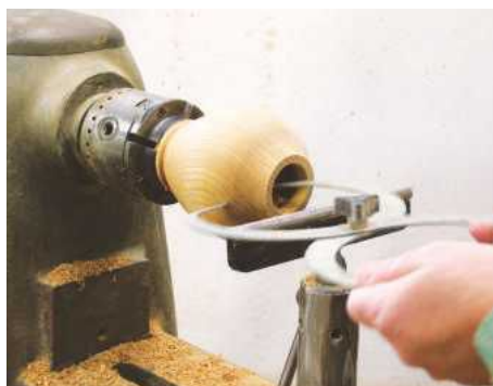
14 Use double-ended callipers to check the wall thickness
