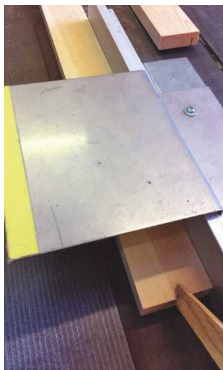
7 Safely rebating the sides under the Suva guard
