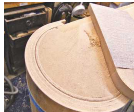
12 Sand the plywood level with the edge of the mould
