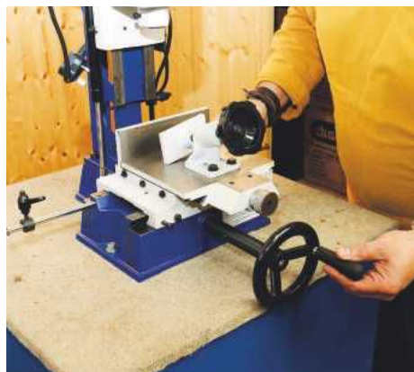
The large front wheel drives a rack and pinion gear to move the timber left and right
