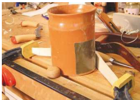
9 ... and a bit of old drainpipe into a former to bend the slat overnight
