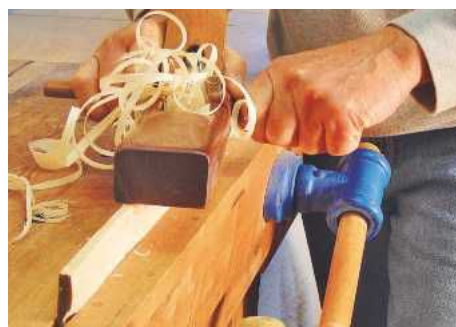
7 A wooden Chinese plane prevented discolouration of the oak
