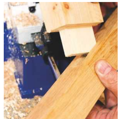
The resulting mortises are clean for a snug fitting joint
