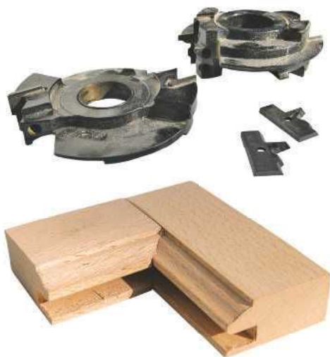
... although I actually used a tenon and moulding combination spindle cutter, shown here
