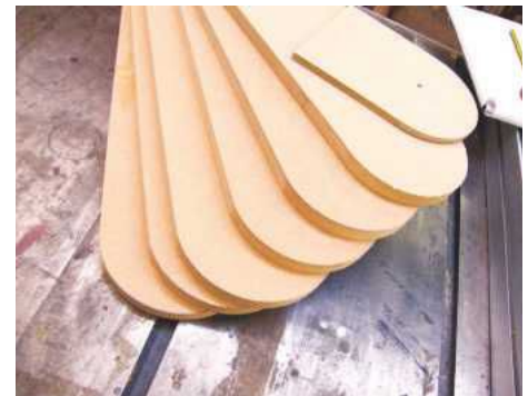
2 Use the template to make six accurate formers for the mould
