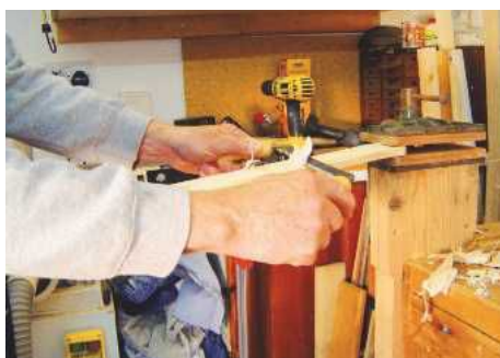
6 ... as well as a conventional drawknife for the final shaping
