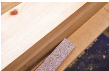
8 The edges are sanded square using a sanding stick
