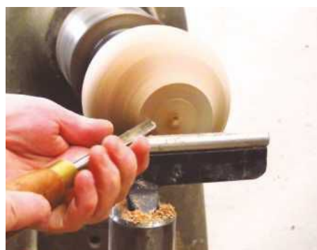
5 Complete the shape of the vase and true up the top
