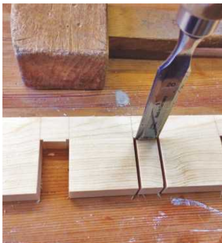
4 ... where some easy chisel work completes the job
