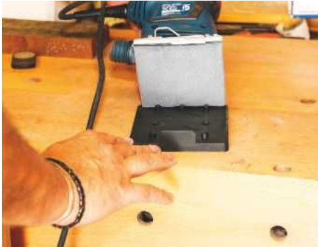
A supplied punch pad is used to allow the dust to be captured
