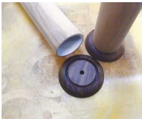
26 Aim for a push fit of the column into the base and top pieces
