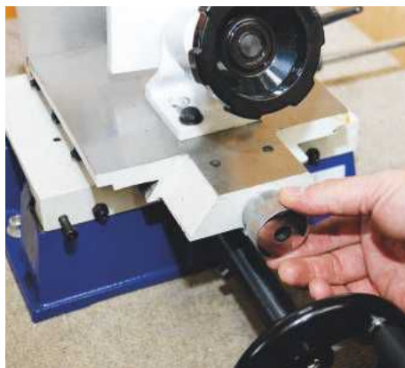
This smaller wheel is designed to alter the backset of the mortise to the fence
