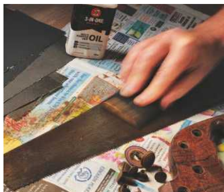
3 Removing rust with silicon carbide abrasive and oil
