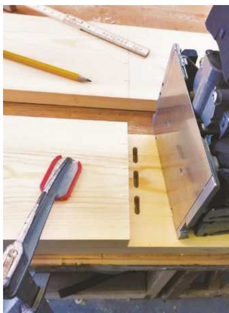
2 Marking out for Dominoes is straightforward enough, but a fair bit of care is required to ensure everything will line up on assembly
