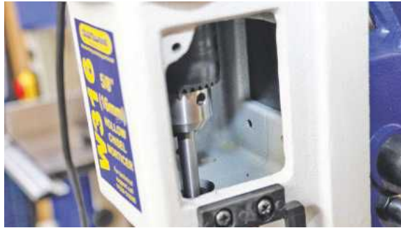
The auger is held in a standard three-jaw chuck
