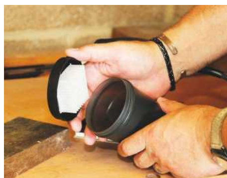
There's a pleated filter fitted to the screw lid, which helps to capture finer dust
