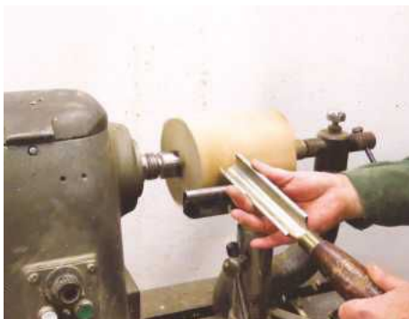
1 Turn the blank to a cylinder using the spindle roughing gouge
