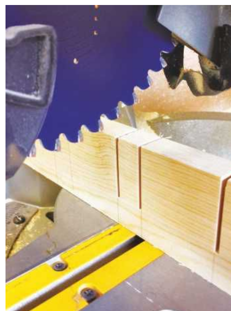
3 Notching out the marking gauge shelf on the chop saw...
