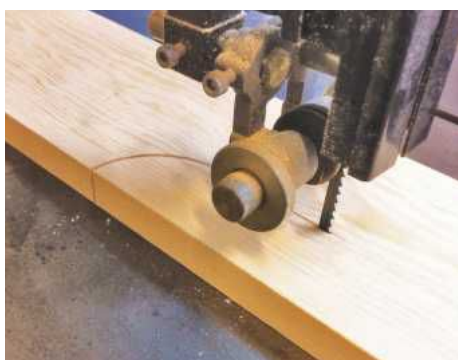
5 Forming the step-down on the lower parts of the carcass sides on the bandsaw...
