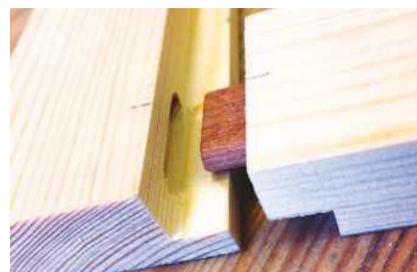
12 The try-out for the stepped shoulder Domino joint for rail to stile
