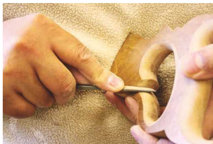
15 The double-ended riffler is great on tighter radii
