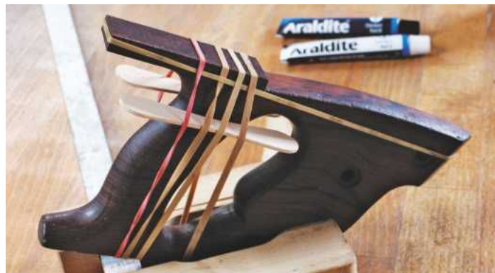
22 Elastic bands hold the repair while adhesive sets
