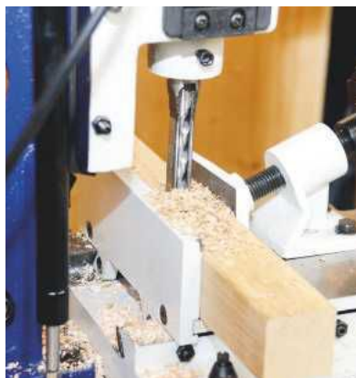
This oak was easy to mortise at its full 16mm chisel width
