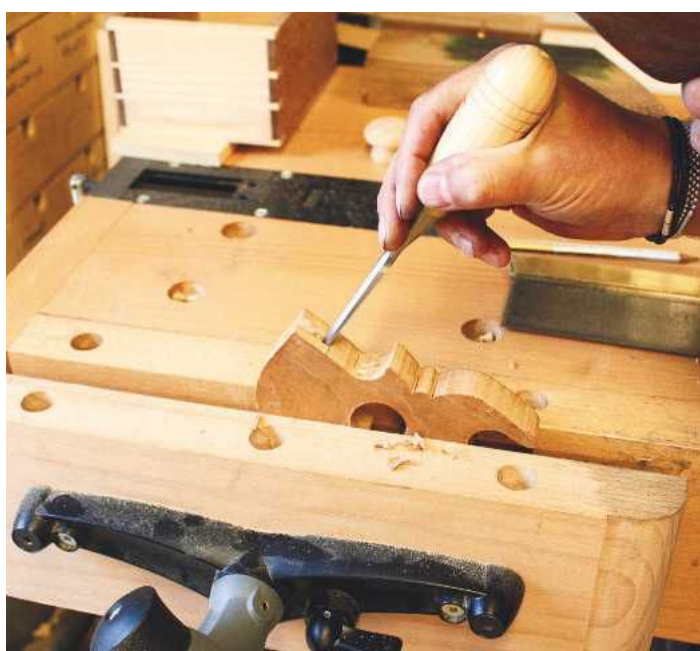
9 ... and chisel the waste away...
