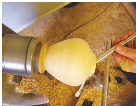
11 The gouge cannot reach underneath the shoulder of the vase...
