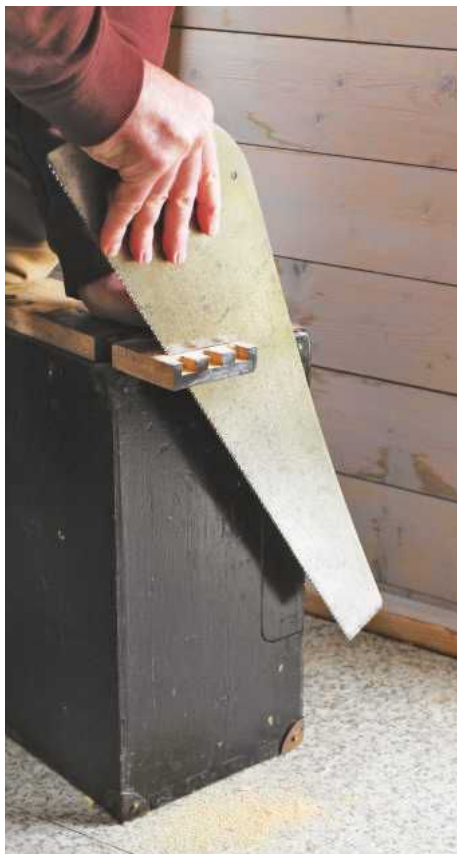
8 First cut with the sharpened blade without its handle
