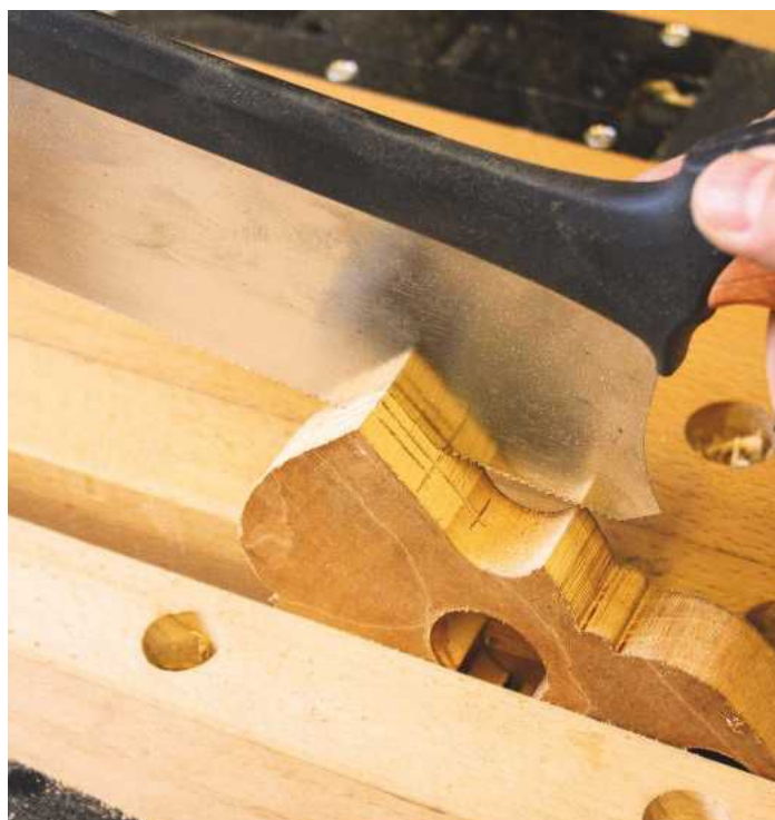
8 ... saw down to the recess edges...
