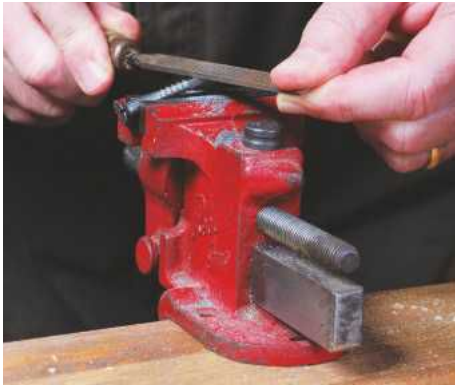
26 Filing a 2in 12 gauge screw to make the 'baby's tooth'
