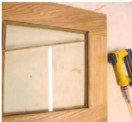
Retaining strips held both the side panels and centre glass panel into their frames
