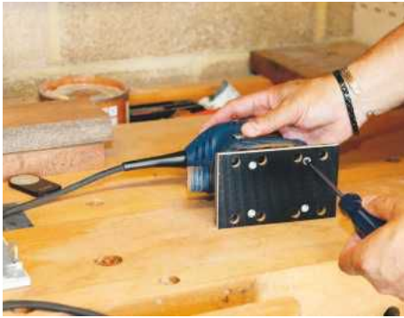
Bases are removed with the supplied screwdriver, which is very quick and easy to do
