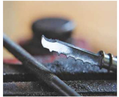
28 A hollow filed above the edge improves performance
