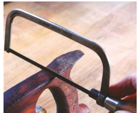
19 Making a stop cut with the hacksaw
