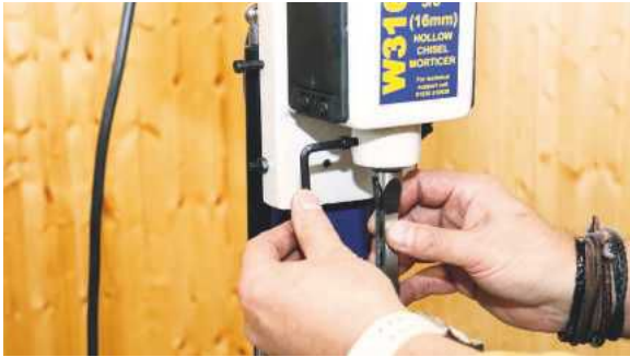
Chisels are secured into the collar with the aid of a hex screw
