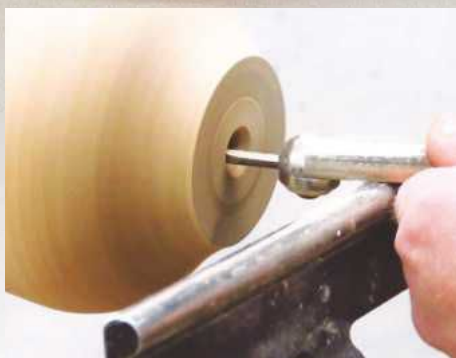
8 Start hollowing by widening the hole using the toothpick
