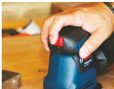
The rubber-shrouded front-mounted rocker is well positioned for easy control
