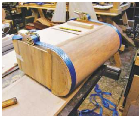
22 Gluing the curve onto the end of the drawer housing cabinet
