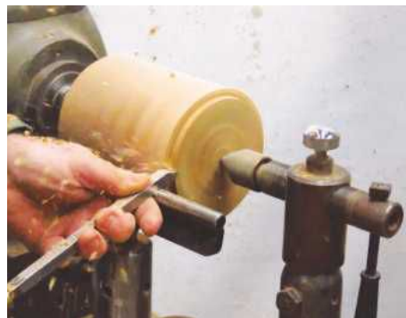
2 Cut a chucking tenon or spigot on one end
