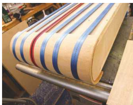
5 The straps are pulled tight evenly
