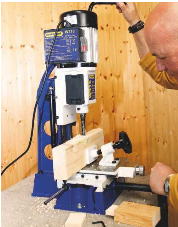
The cranked handle works well for longer plunges
