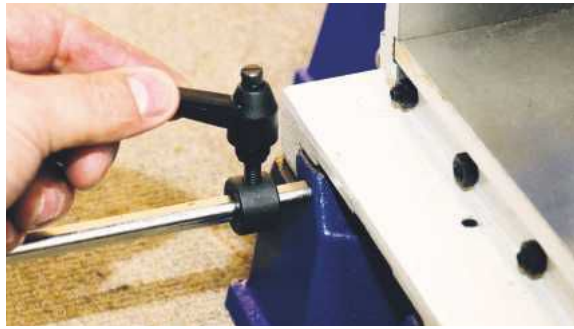
Similar stops can set the mortise width for fast repeat work
