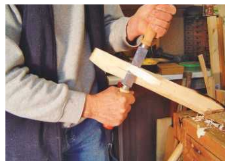
5 Shaping was done with a Swedish drawknife, specifically designed for green wood...
