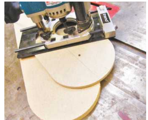
1 Make one accurate template using MDF
