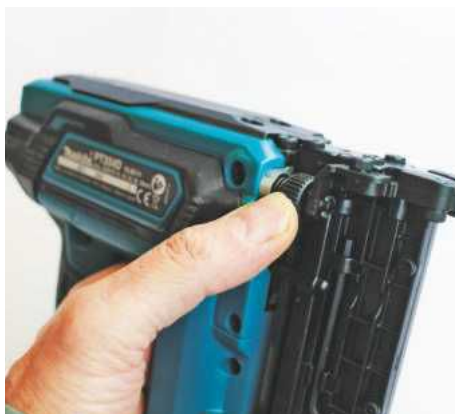
This knurled thumb-wheel controls the depth of pin set
