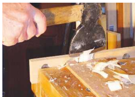
4 ... and a trimming axe to prepare a blank
