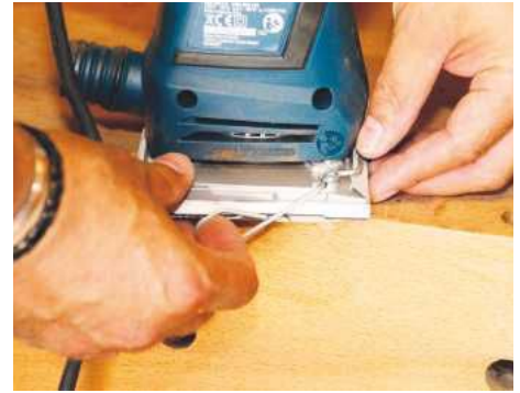
The small square base has simple wire clips for standard abrasives
