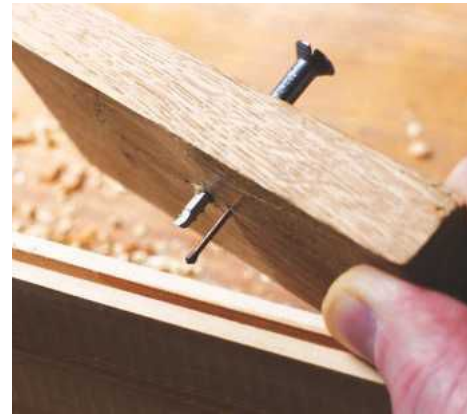
31 The screw thread makes the cutter adjustable for depth
