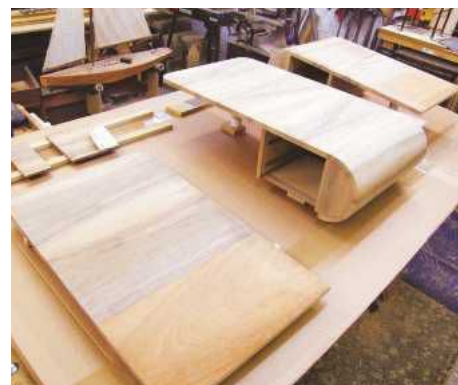
24 The individual components ready for finish sanding and varnishing
