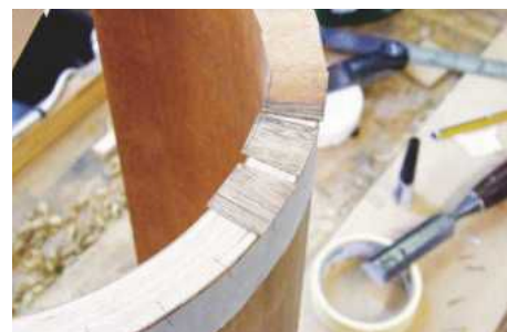
18 Small wedges of veneer are glued around the perimeter
