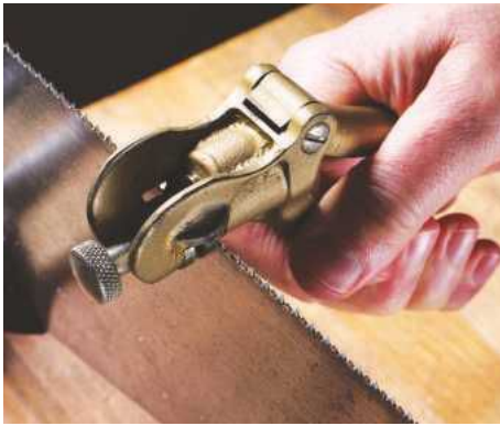
14 Setting teeth with the Eclipse 77 saw set
