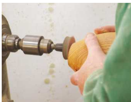
23 Sand the stub away using a sanding arbor in a Jacobs chuck
