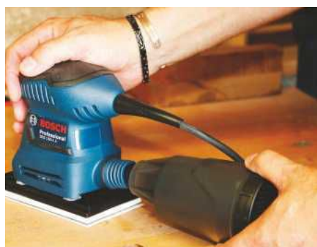
A simple push fit over a rubber 'O' ring firmly secures the dust collector
