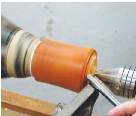
22 Reverse chuck the base to remove the chucking point
