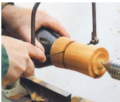
5 Alternatively, cut the lid off with a saw
