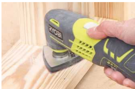
28 Clean off excess glue from the joints and sand the cabinet inside and out using 180 grit or finer abrasive
