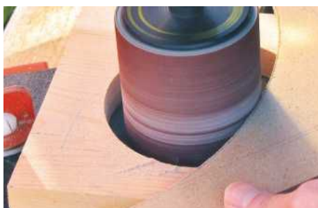
9 Cut carefully with a jigsaw and tidy up the template curve with a sanding drum mounted in a drill stand
