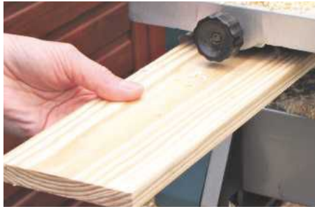
19 Reduce timber thickness for the drawer to around 15mm. Cut front, back and sides to size
