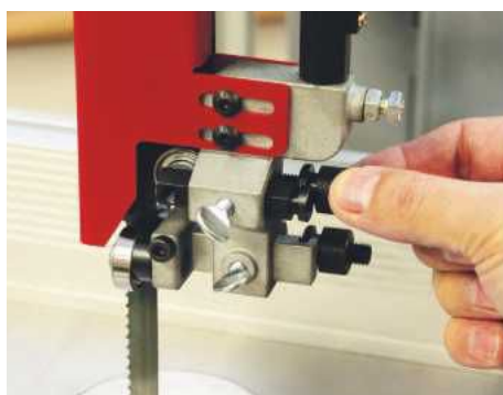
The upper guides are adjusted without the need for tools
