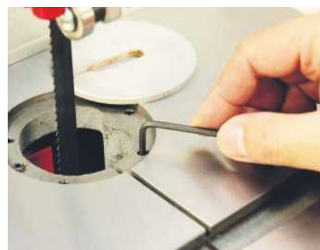
Height adjusting screws allow the insert to sit perfectly flush
