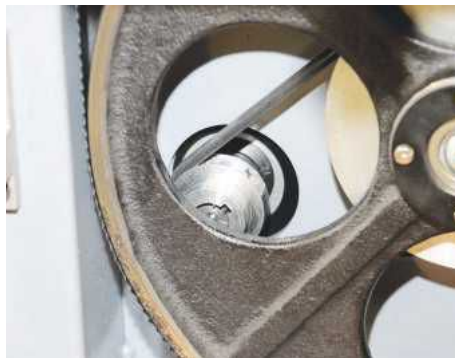
You swap the belt to alter to either of the two speed ratios
