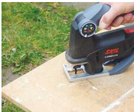
Testing the saw on 12mm MDF. The Combisaw copes better cutting thin sheet materials than thicker timber
