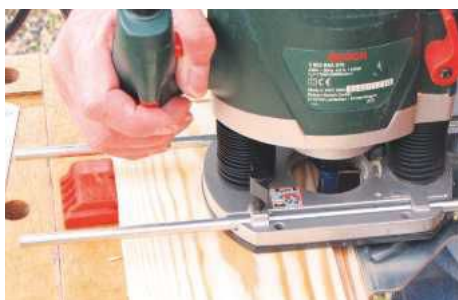
3 Rout a 15mm-deep rebate along rear edges for the matchboard back panel. The rebate is stopped on the top and bottom
