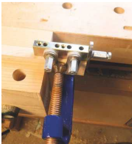
5 ... so that the Joint-Genie can register against the end of each piece
