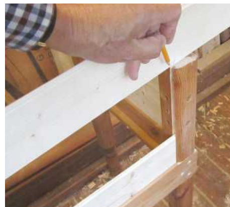
8 Making the outside faces of the rails and legs flush meant that all the trenches for the panelling could be cut with a single router setting
