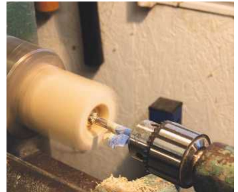
7 Drilling an additional 15mm hole to a depth of 70mm
