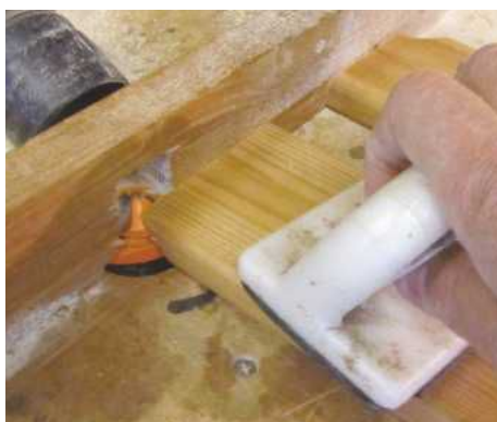
5 A drawer-cutting router bit helped to strengthen the corners where the lower rails met...
