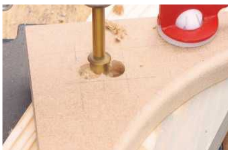
16 Using a 15mm Forstner bit, add decorative trefoils to the top corners
