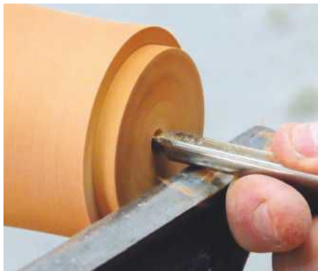
13 Bore a hole down the centre of the box using a spindle gouge...
