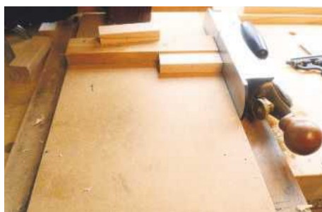
4 All the door stiles and rails are shot to precise length...
