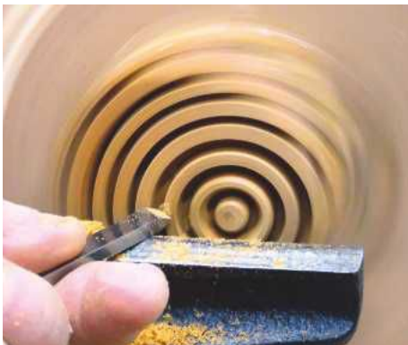
12 Round over the top of the rings with a skew chisel
