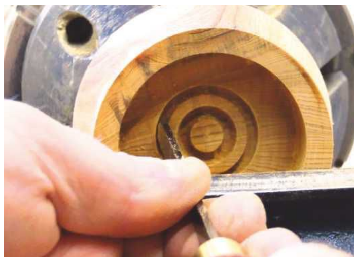
8 Use a small parting tool to cut concentric rings in the lid
