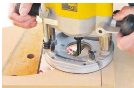
14 Using a flush-trim cutter with the bearing running against the template, rout the MDF panel
