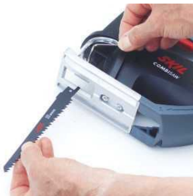
As a recip saw, fitting a standard straight blade (with hook and pin shank) poses no problem
