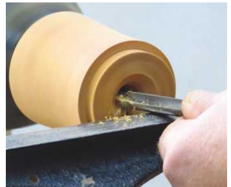
14 ... and hollow from the hole, working outwards
