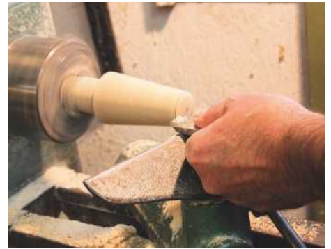
13 Forming the cushioned top with a scraper
