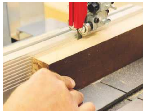
Thin repeat veneer cuts are accurate and consistent
