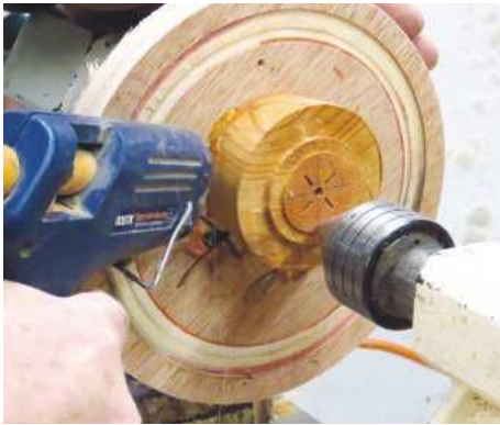
9 Glue the lid to a plywood disc, offsetting it a little
