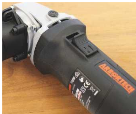
The excellent on/off switch; the side handle fits in just above, or on the other side
