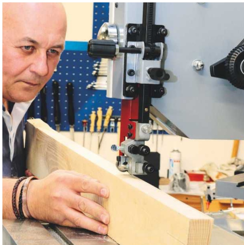
The saw is equally powerful for deep ripping of timber
