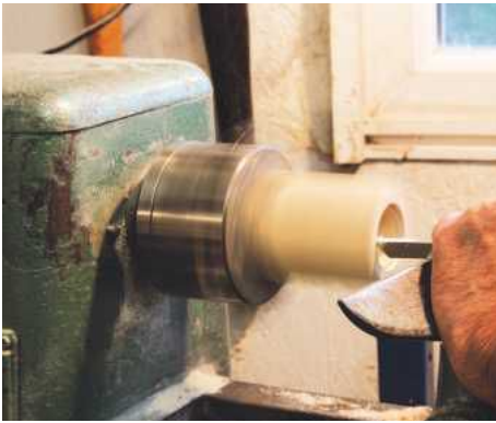
20 Using a bedan to cut the shallow rebate to accommodate the shoulder of the bung
