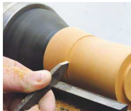
3 Use a parting tool to cut the tenon on the base...
