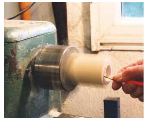
19 Marking with a pencil with the bung inserted
