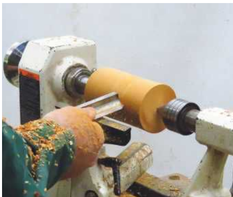
1 Turn the blank to a cylinder using a spindle roughing gouge
