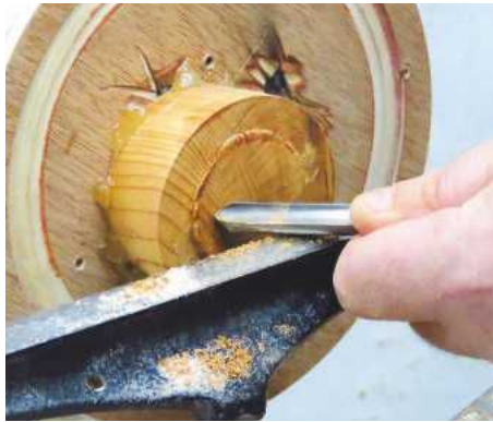
10 Remove the chucking spigot and clean up the top of the lid
