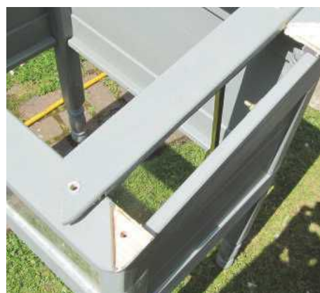
13 Unscrewing two bolts allows the glass to be slid in after painting, which makes for a cleaner finish. It also allows a broken pane to be replaced easily
