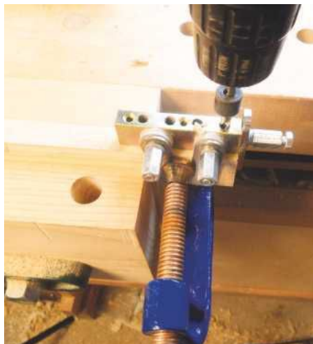
6 You'll need a drill with a depth stop to make quick, perfect and invisible dowel joints with the Joint-Genie
