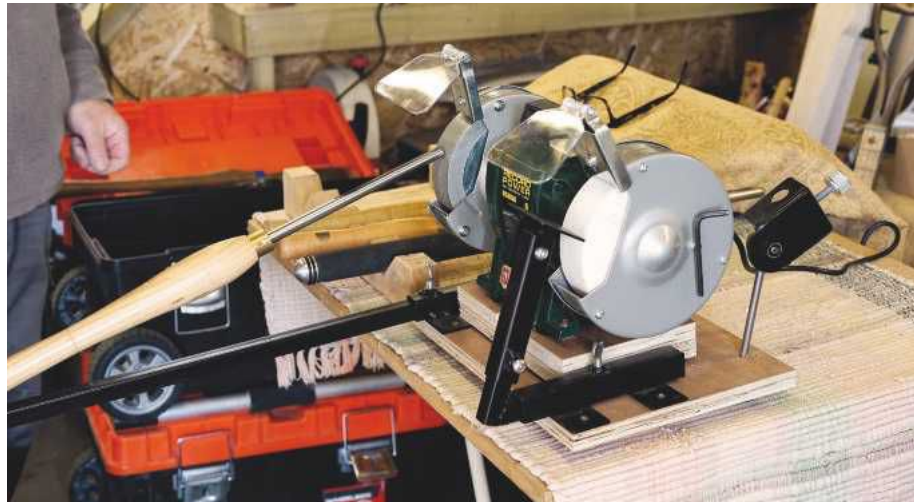
1 Sharpening tools using a jig
