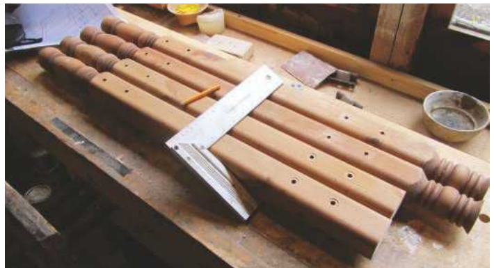
2 Once the legs were cut to length, lining up the feet allowed me to mark up a reliably level position for the lower rails
