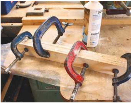
2 Strips being glued and clamped
