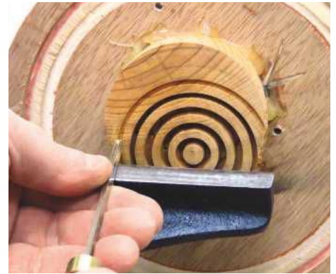
11 Cut a series of concentric rings using the small parting tool
