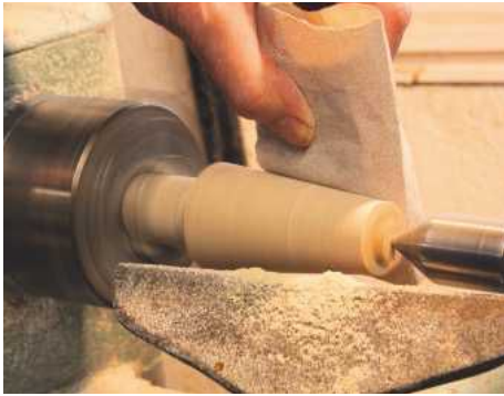
11 Sanding the external taper – working through the various grits
