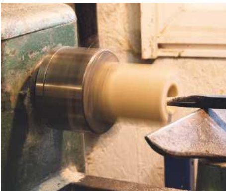
8 Turning the internal taper with a carbide tool
