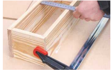
23 Dry-assemble the drawer and carefully measure for the bottom panel. Cut this about 2mm undersize
