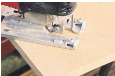
11 Saw the arch from the MDF front panel, keeping it at least 2mm on the waste side of the line
