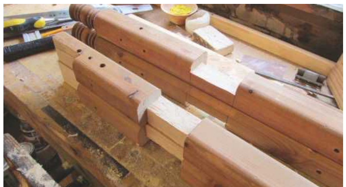
4 The hardest part of preparing the legs was making sure that all the joints were on the right faces
