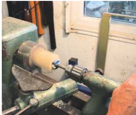
6 Drilling out with a 35mm Forstner – note tape showing depth of cut
