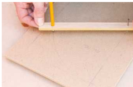
8 Construct a template from 6mm MDF. Make a trammel from scrap and mark out an arch radius of 175mm
