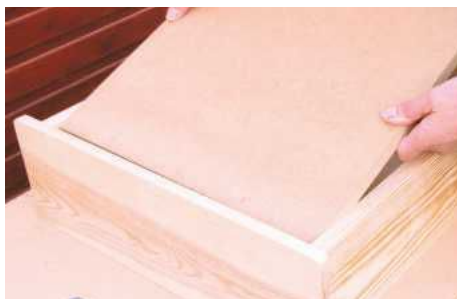
7 Saw the MDF front panel and trim edges until it fits snugly. This will be cut out to create the arch
