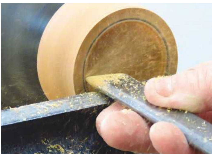
7 ...then use a skew to cut a parallel side wall
