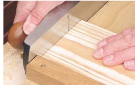
20 Trim ends square on a shooting board if required. Mark and cut slots for smaller, No. 10, biscuits
