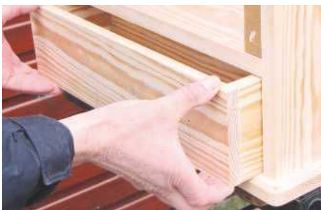
27 Check the drawer fits into the cabinet neatly. Adjust if necessary by trimming the ends with a finely-set plane
