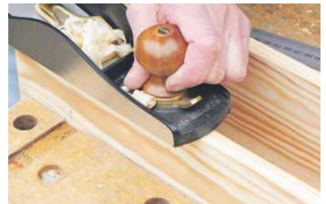
26 Clean up the upper and lower edges of the drawer, checking with a straightedge. Avoid breakout on the corners
