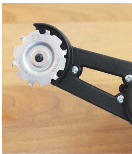
The Arbortech Pro blade is frighteningly efficient at removing timber stock at speed
