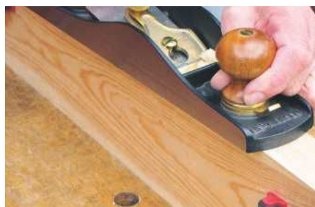
5 Cramp top and bottom panels together and lightly plane front edges to clean them up, if necessary
