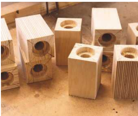
17 Remaining blocks drilled with a stepped hole
