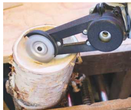
The smaller blade of the mini system enables tighter access for any kind of shaping work
