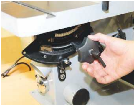
Rack and pinion gearing make tilting the table easy
