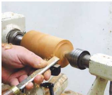
2 Cut a chucking point on both ends of the blank
