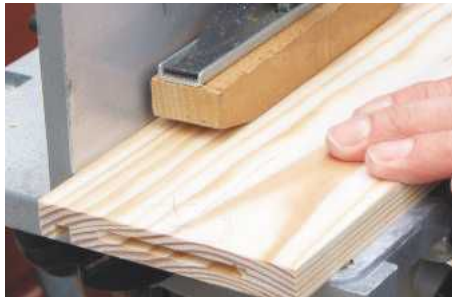
22 Rout a 7mm-deep groove for the bottom panel along lower edges of the front, back and sides
