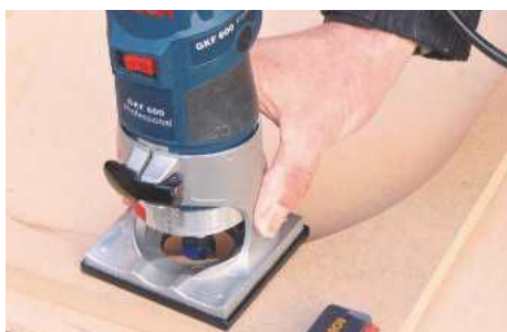
15 Either round over or chamfer the front edge of the panel with a bearing-guided router bit
