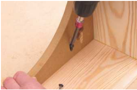
18 Cramp and screw the panel into the cabinet, setting it back 2mm from the carcass' front edge
