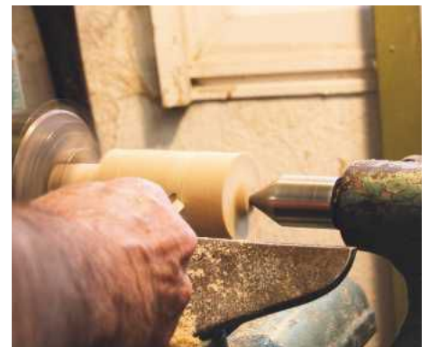
10 Turning the external taper on a jam chuck – note point of live centre covered by plug
