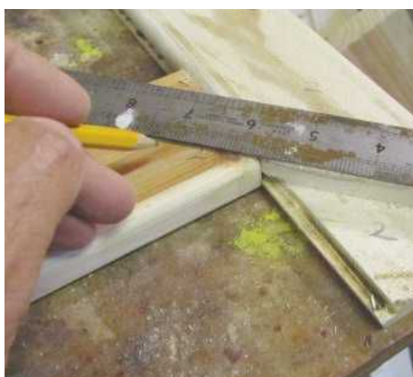
12 Marking each half of the lid's joints from its mate ensured that small mistakes in the cutting angle didn't matter. Numbers kept matching components together
