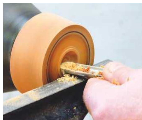
6 Hollow the lid with a spindle gouge...
