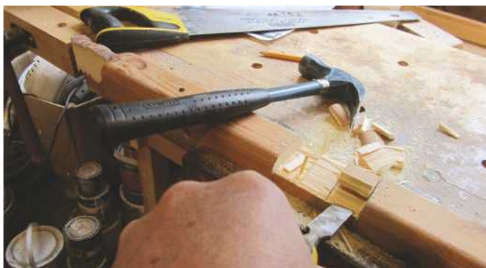
3 The housing joints needed to be a snug fit to hold the rails square, but because they're deep they didn't have to be perfectly flat across the bottom
