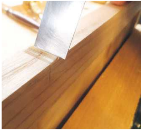
12 A mallet and chisel, held bevel down, loosens the bulk of the waste..
