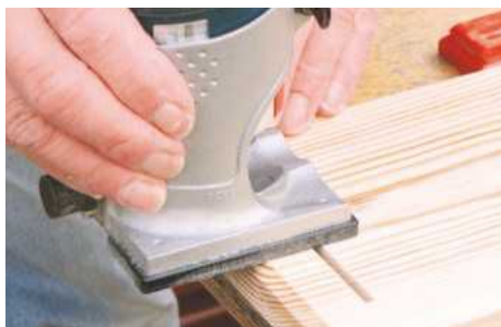
6 Chamfer upper and lower edges with a bearing-guided bit, then glue up carcass, checking for square
