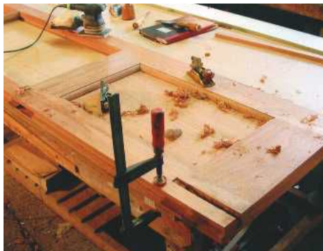
6 A door being fitted with a large 200mm polished brass flush bolt – not an easy thing to do
