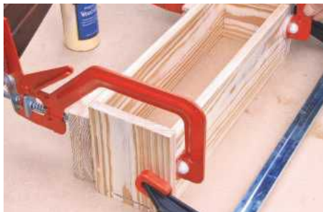
25 Glue the drawer together, though avoid gluing the bottom panel. Cramp and check for square
