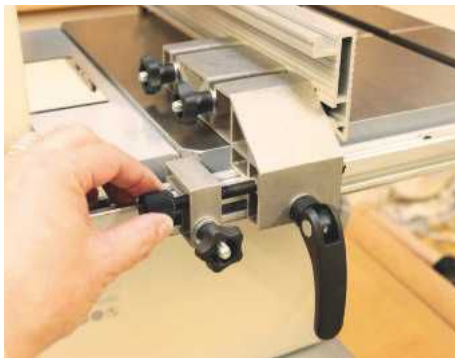
The fence locks with a cam lever and has a fine adjuster built in
