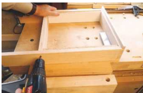
3 With the dovetailed end in place, the divider is simply screwed into position, located against strips of scrap
