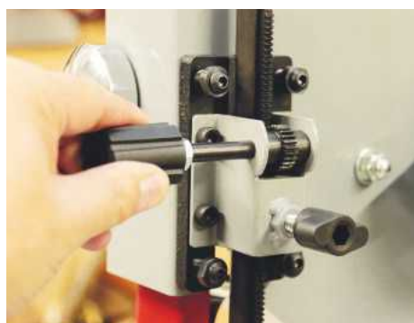
The depth of cut is altered with this heavy-duty rack and pinion setup
