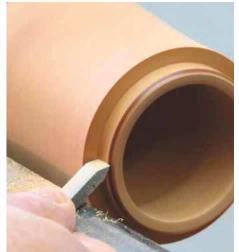
20 Cut the tenon down to the burnish line for a good fitting lid
