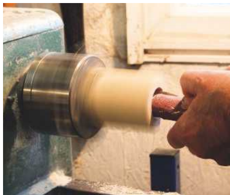
9 Sanding the inside taper with a wooden dowel inside some abrasive roll
