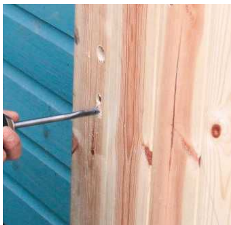
Fitting locks with these flat bits is ideal for finer spindle and key hole drilling
