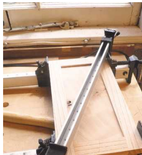
7 The first door in the cramps: a clamp across the diagonal is a great method of fine adjustment for squareness
