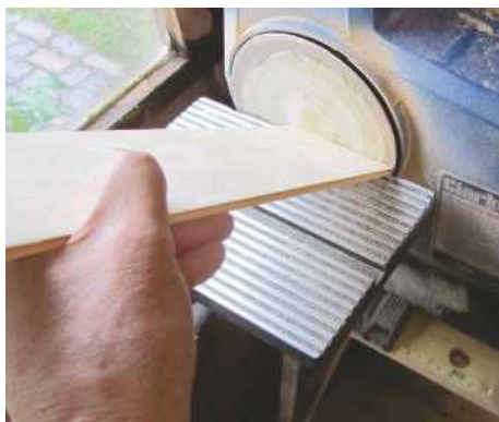
9 Sanding the ends of the tongue-&-groove boards allowed them to slip easily into the trenches. The boards were glued to each other but not to the frame
