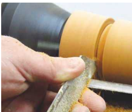
4 ... and a narrow parting tool to separate the base from the lid
