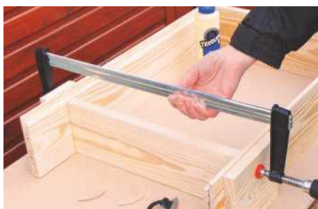
4 Assemble the drawer divider and sides with PVA glue and cramp up. Use the drawer front as a spacer at the far end
