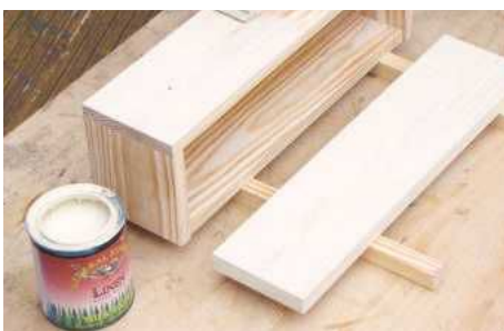
30 Brush on at least two coats of a suitable paint, sealing the MDF first
