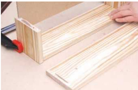
24 Check that the 6mm-thick MDF panel slides into the drawer and everything fits together snugly
