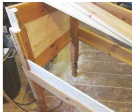
10 The rails were glued and screwed to the legs; the holes left over from the flat-pack bed were filled. Ledger strips support a loose plywood floor
