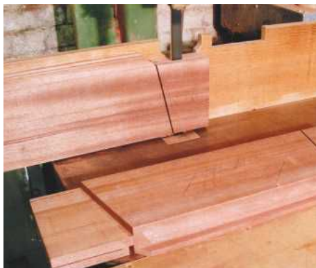
3 Bandsawing the cheeks of the tenons
