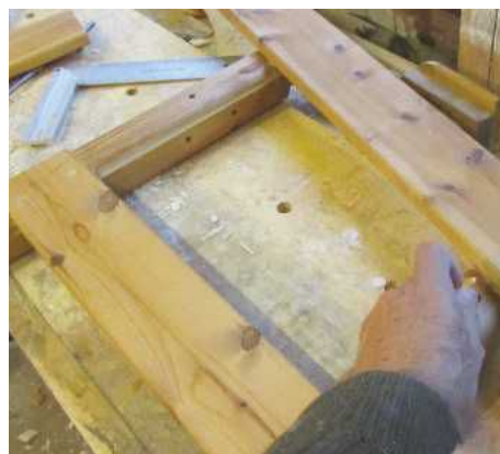
7 With the lower rail temporarily screwed into position, marking up the length and angles for the top rail required no calculation
