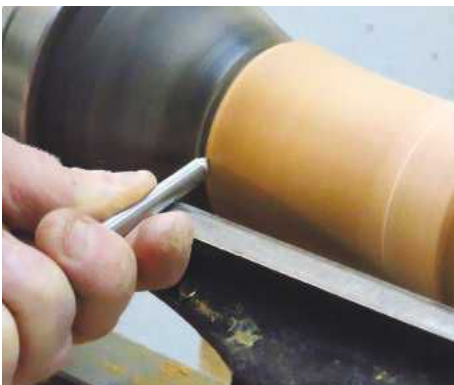
21 Finish shaping the outside of the box
