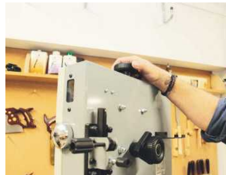
Blade tension and tracking are set using the top and rear knobs
