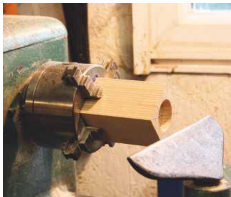
18 Remounted in the engineer's chuck
