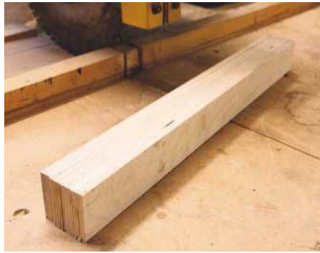
3 Planed batten of birch ply
