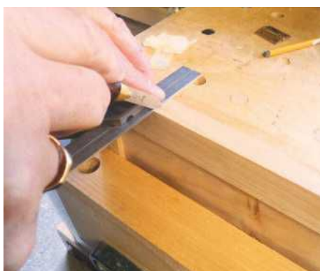
10 Hinge housings are marked with a knife...
