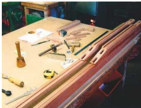
5 A pair of stiles awaits the rail's guide
