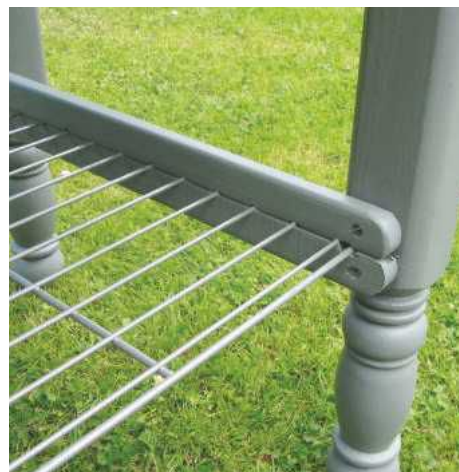
16 The shelf supports were made from grooved decking offcuts. Notches (quickly cut with a bandsaw) stop the shelf pulling free even under heavy load
