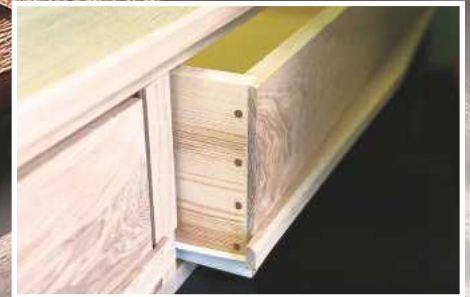
Dowelled with contrasting timber, lap joints look good with drawer sides
