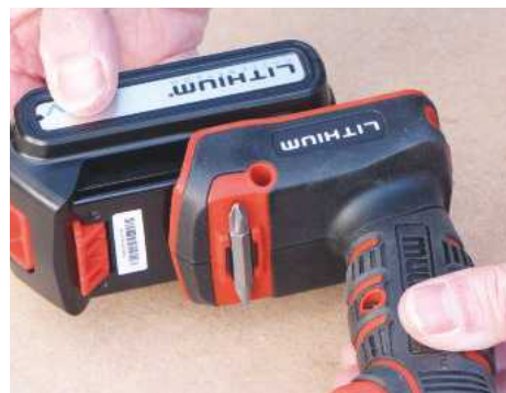
The drill's 18V cells are powered by a 1.5Ah Li-ion battery, and you have two of these with a charger
