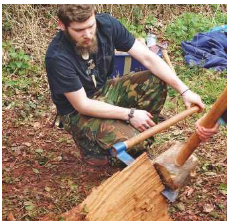
A froe being hammered into end-grain
