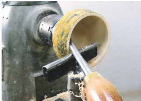
20 Here you can see the rim of the bowl interfering with the shaft of the tool
