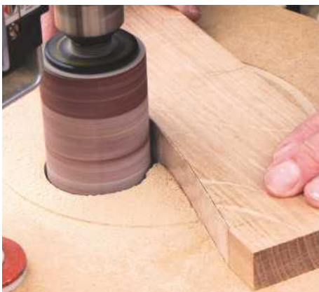
9 Saw the curve just on the waste side of the line and clean it up on a sanding drum
