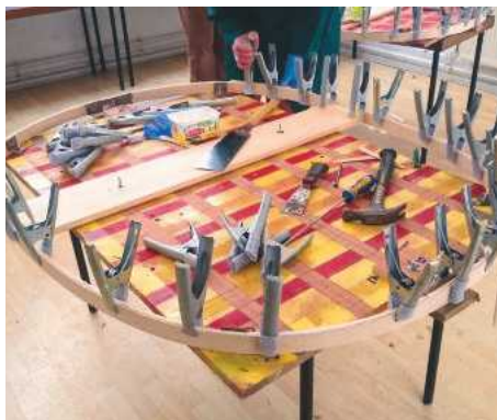
1 Laminating the gunwale trim with the seat fixed across the jig
