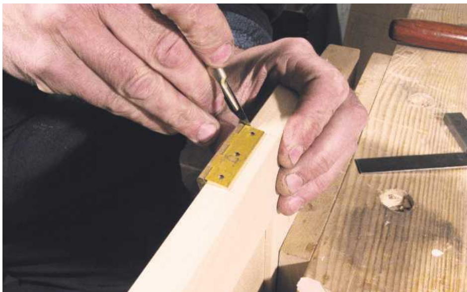
6 Repositioning the hinge, prick with a scalpel or marking knife then mark around
