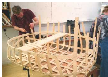
6 Trimming off the laths and stringers
