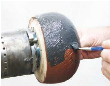
16 ... followed by two coats of metal reactive paint
