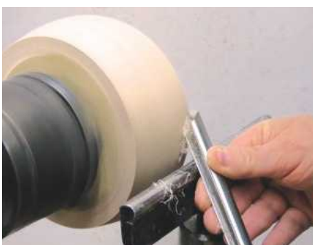
7 Final shaping and finishing is carried out using the wing of a swept-back bowl gouge
