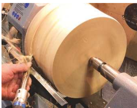
STEP 2 Start by mounting the bowl blank on the lathe and true up the surface using a 12.5mm bowl gouge
