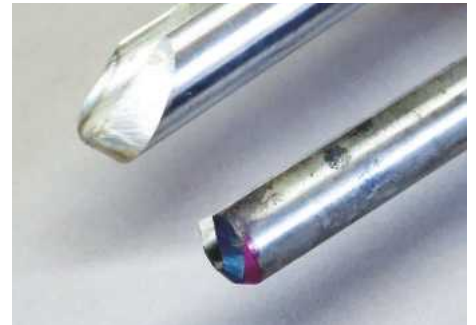
21 Shortening the bevel on the bottom tool...
