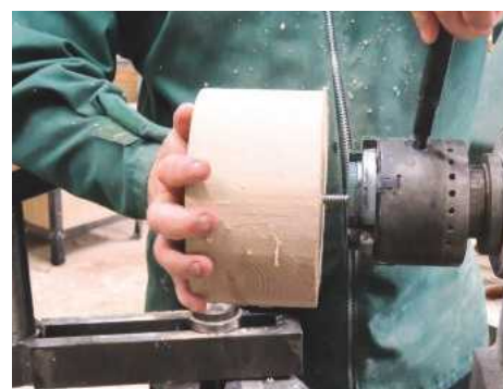
1 These machine screw chucks require an 8mm hole to be drilled in the blank
