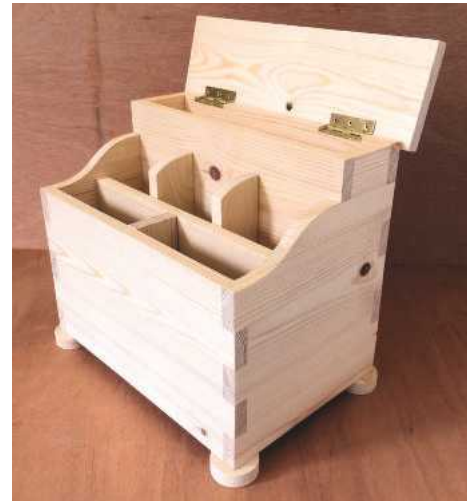
14 The hinge recesses were routed out with the very handy Bosch palm router
