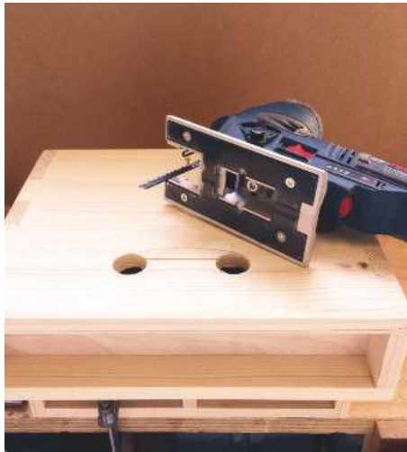
13 With the handle holes drilled, it's fairly straightforward to form the final shape. Note initial halving cut on the waste
