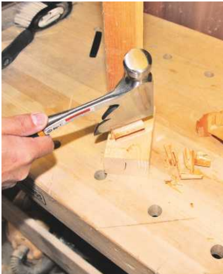
Cutting a twisted plug is a classic use of an axe, chopping opposing corners
