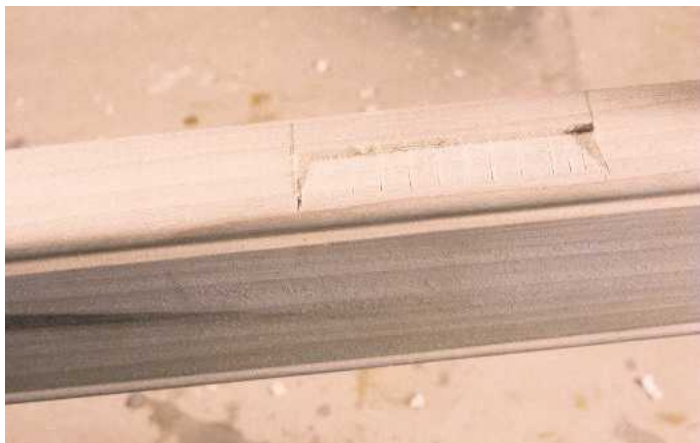
17 Complete the recess by chopping the slivers from the end knife lines
