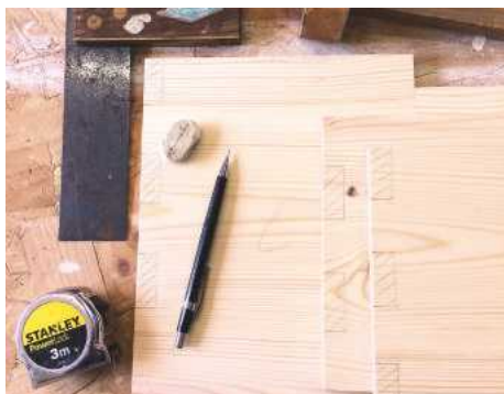
3 Make your marking out as clear and accurate as possible
