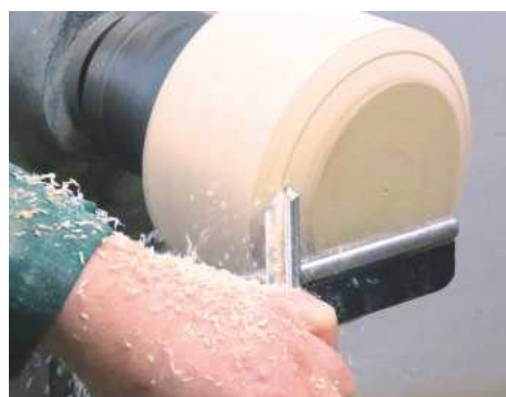
3 Start shaping the outside of the bowl using a bowl gouge
