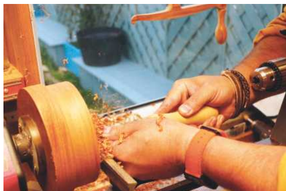
The short length allows easy access without removing the headstock
