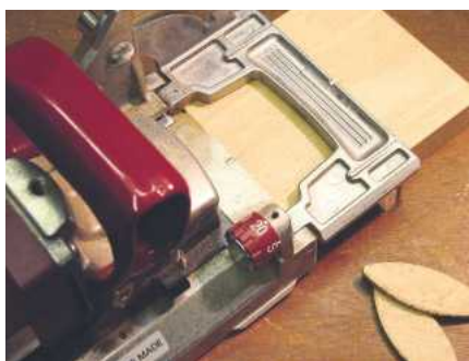
Biscuit joints are quick and efficient to make
