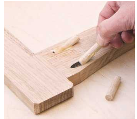
17 If jointing with pocket screws, glue plugs into the recesses. When dry, saw the plugs flush
