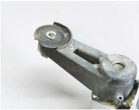
10 My mini Arbortech in an angle grinder that I use for texturing
