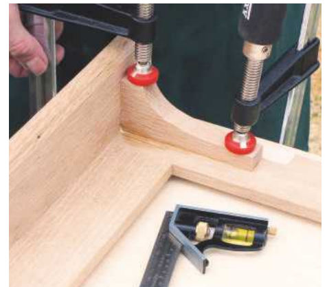
20 Glue the brackets to the stiles, checking that each one is central. Masking tape reduces glue clean-up
