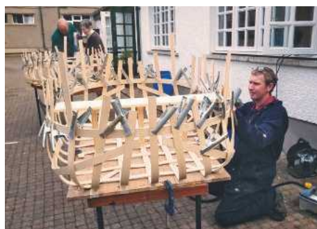
5 Adjusting and checking alignment of the ribs and stringers
