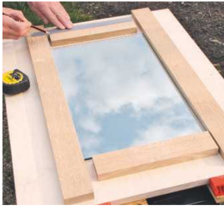
4 Laying out the components will help you decide how figure and grain patterns are displayed to their best
