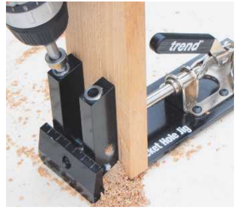
5 Using a pocket hole jig, drill both ends of the top and bottom rails for the fixing screws
