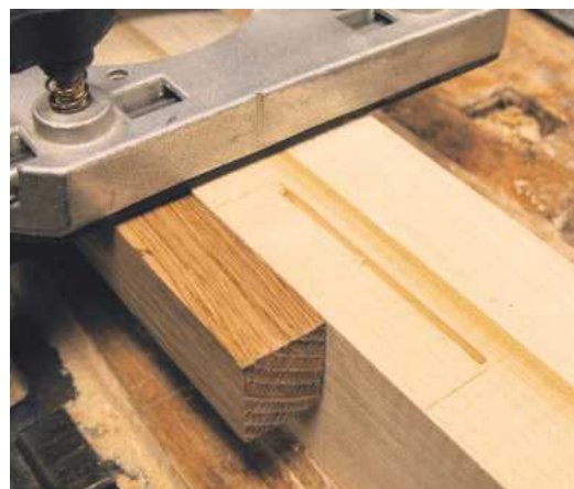
21 Rout out a groove at the back of the recess, leaving a good clean line
