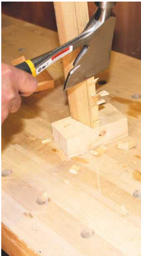
Start from the bottom and work up in a series of small controlled chops
