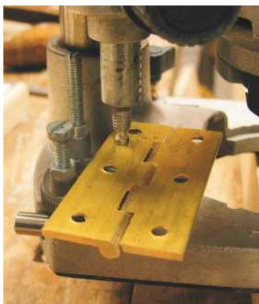
20 Set the depth to the thickness of the flap by inserting the flap into the depth stop
