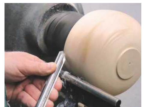
9 Always cut from small diameters to larger on the outside of a side-grain bowl
