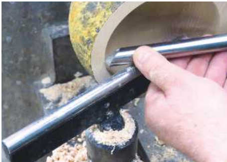
19 ... but when you near the rim, the tool has to be swung right over the lathe to allow the bevel to follow the outside profile
