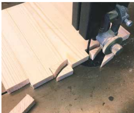
4 The bandsaw remains the easiest way to cut this type of joint
