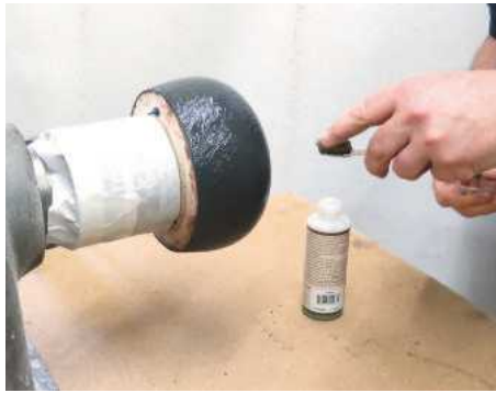
17 Spatter or spray on the reactive chemical before the second coat dries
