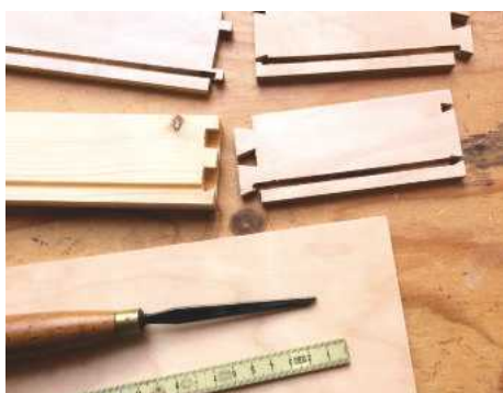
10 The various components of the drawer, cut and grooved
