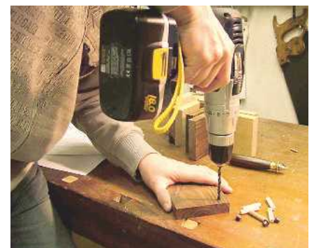
Dowels are stronger than biscuit joints, but trickier. Here the drill must be kept perfectly square
