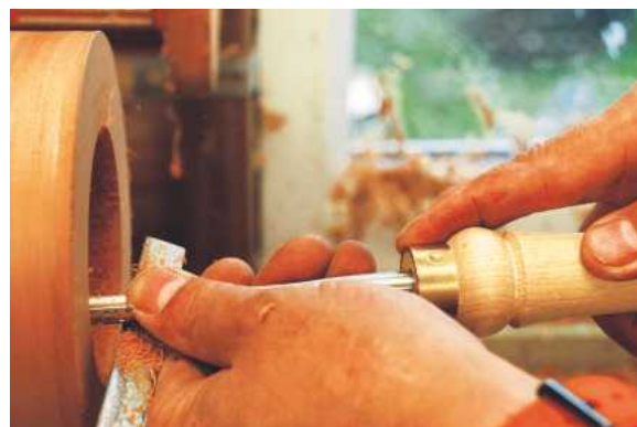
Taking deeper cuts can be strenuous on the wrist so a finer cut works best
