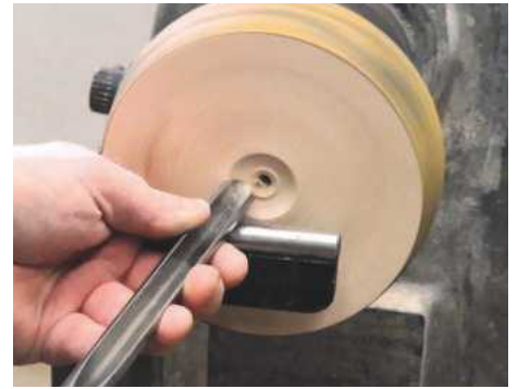
18 Initial hollowing is carried out as normal...
