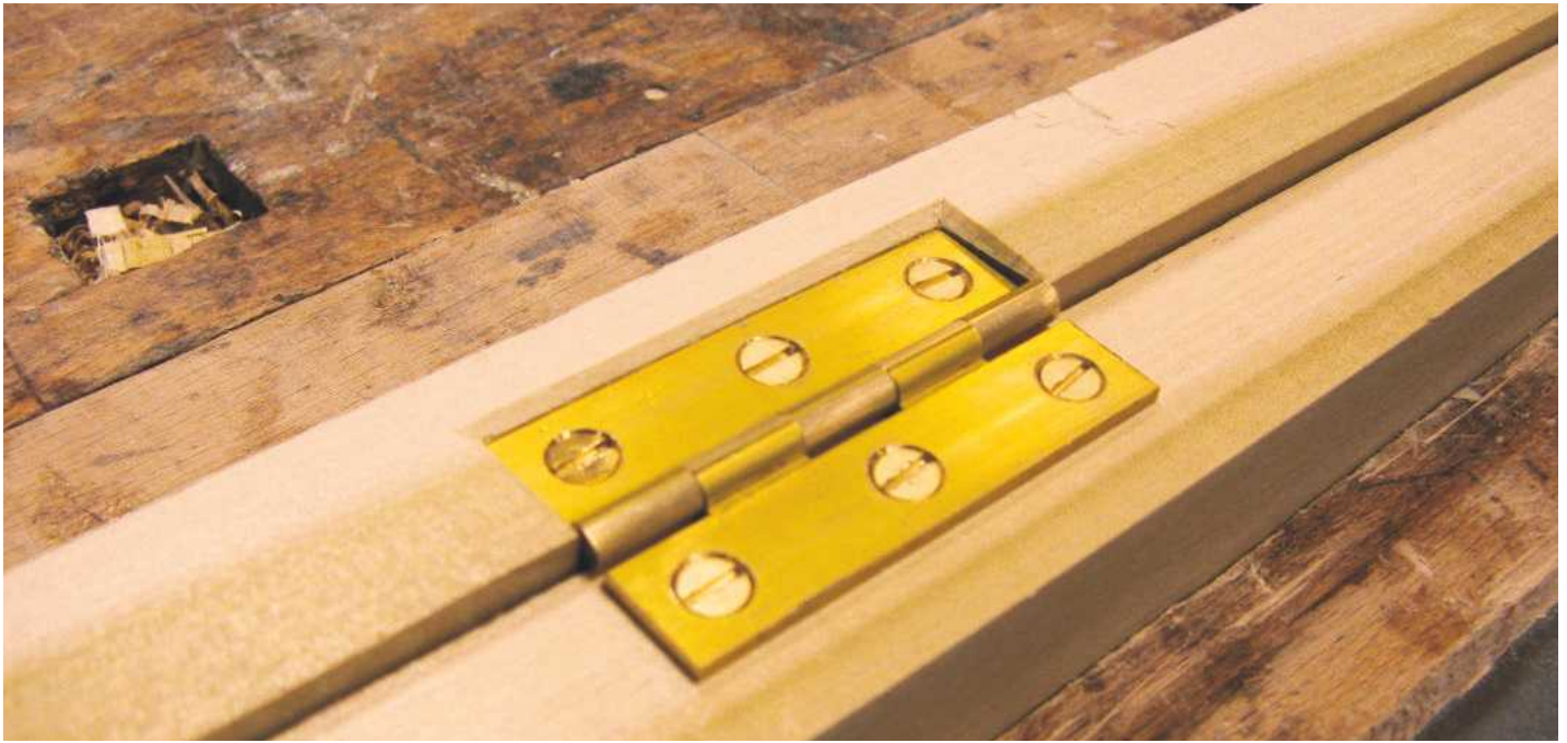
1 A traditional method is to recess the hinge entirely into the door stile, but the recess has to be chamfered to avoid binding and it has to rely entirely on the screws for support
