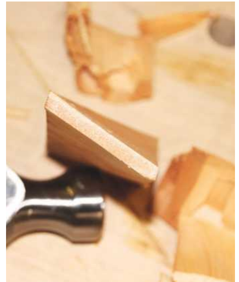
The resulting plug should have a propeller-style twist when viewed on end
