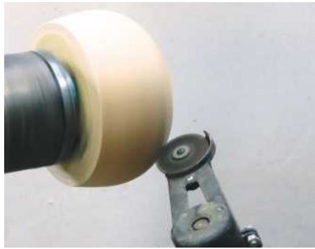
11 Brush the blade lightly against the revolving wood...
