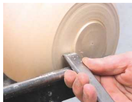
4 Cut a suitable spigot for your chuck
