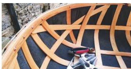
10 Fixing the outer gunwale rim with boat nails and rove
