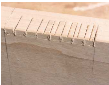
8 Break up the waste with a sharp chisel and then pare away
