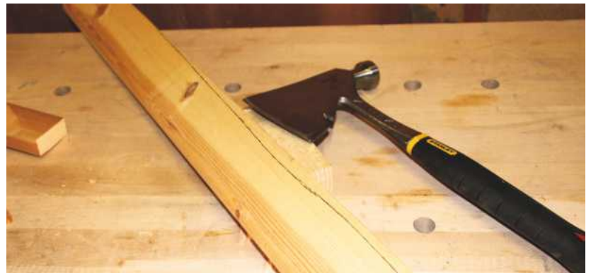
Scribing work such as this architrave is another classic use for a hatchet
