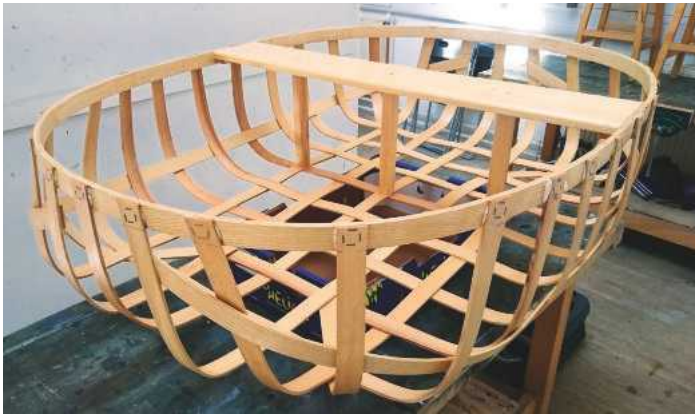
8 The completed frame before covering
