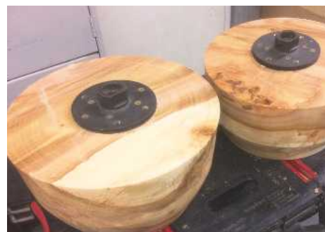
STEP 1 The bowl blank you use should be held in place either using a faceplate or screw chuck
