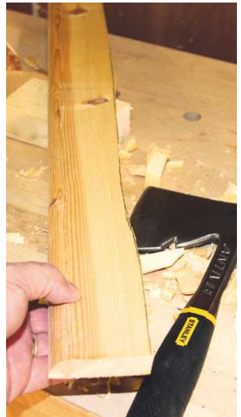
Controlling the axe in small chops will allow you to scribe to a line easily
