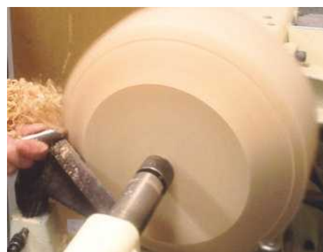
STEP 3 Continue the turning process until you are left with a cone shape
