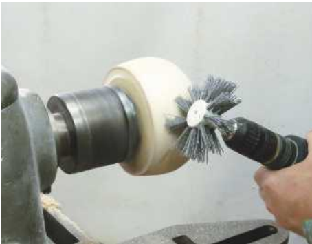
13 You can then clean up the surface using a nylon rotary abrasive
