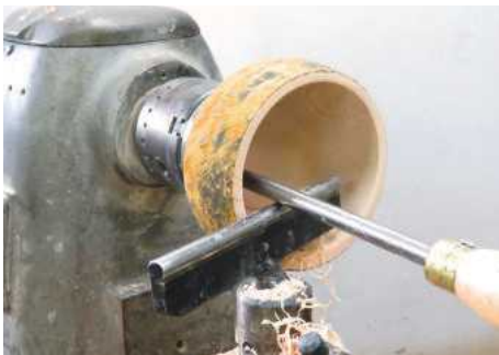
22 ... allows full bevel support without the shaft hitting the rim of the bowl
