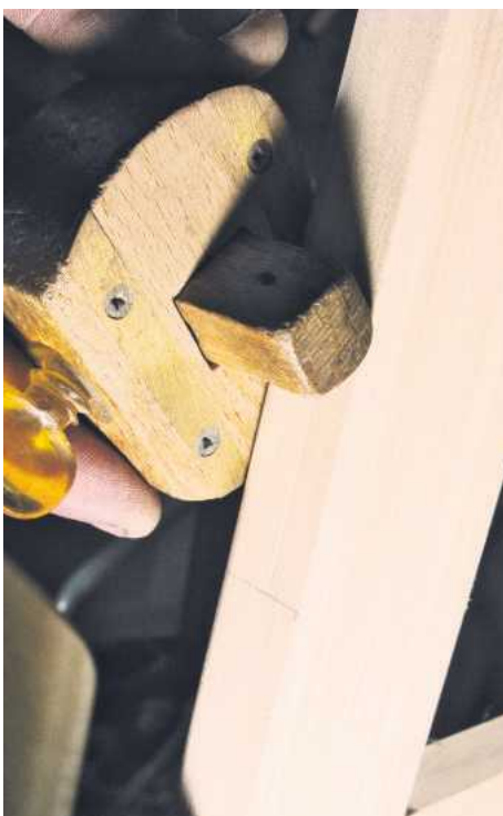
14 ... and then mark the width of the recess between the pencil lines with the marking gauge
