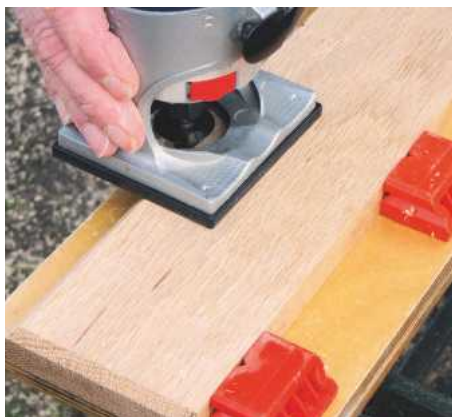
10 Rout 5mm chamfers around the lower ends of the stiles and along the top shelf
