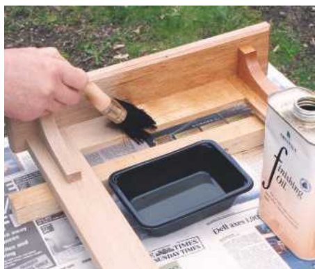
22 You are then ready to dampen the oak and lightly re-sand the surface. Finish with two coats of oil, followed by wax
