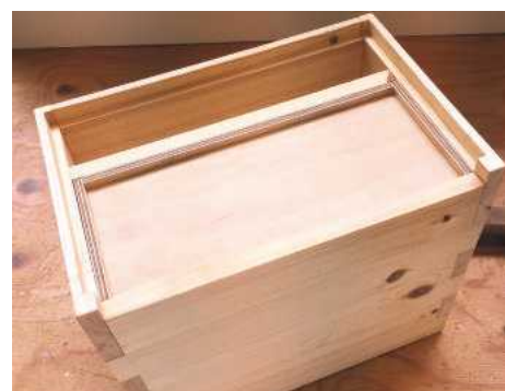
12 A very good fit for the drawer was aided by the access provided by the bottomless carcass
