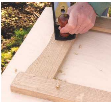
13 You can now true up the surface of the frame, checking for grain direction. If the wood tears, use a cabinet scraper
