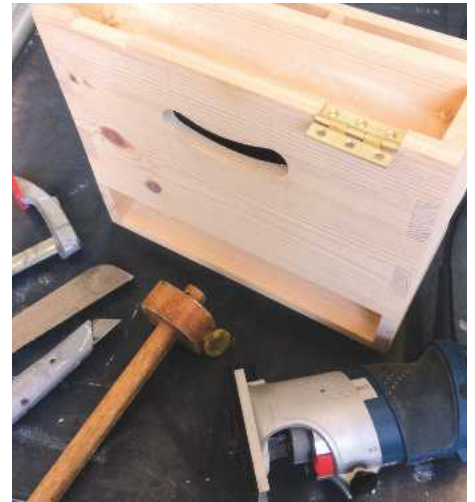
14 The hinge recesses were routed out with the very handy Bosch palm router
