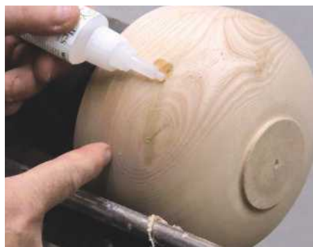
6 As you can see here, I filled a small split with dust and CA adhesive
