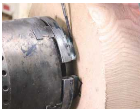
2 Make sure the blank is located firmly against the base of the screw chuck
