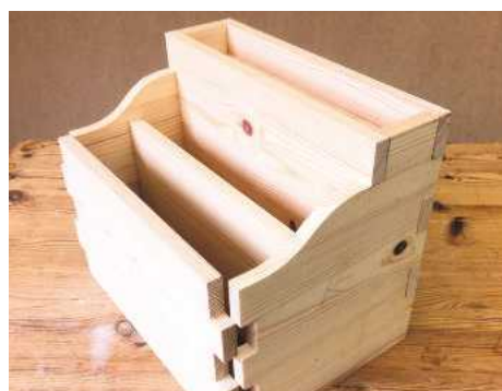
8 The dry assembly is one of the most important parts of a job
