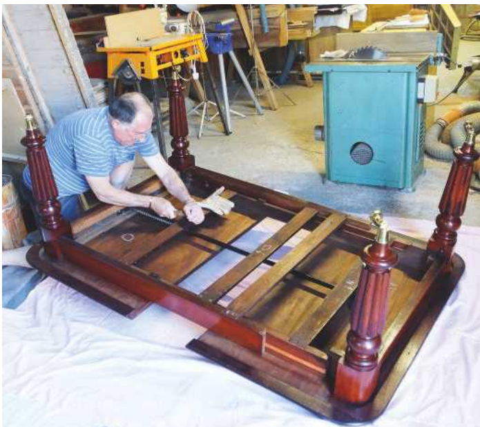
20 The last bit – fixing the winding gear in place
