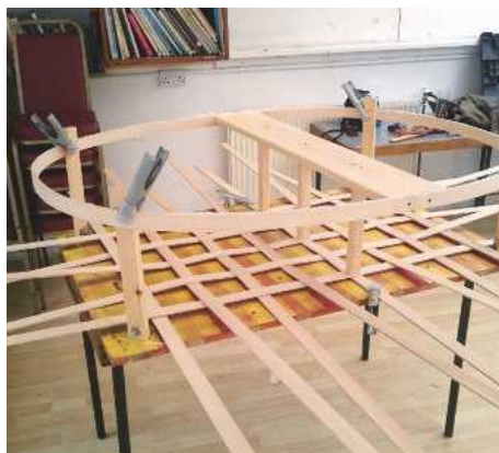
3 Completed rim fixed above the woven hull on temporary corner posts
