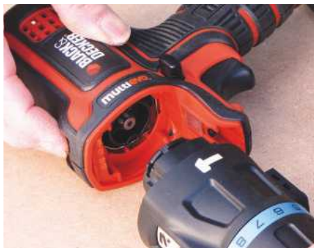
The chuck and gearbox are very easily unlocked and clicked back for head changing
