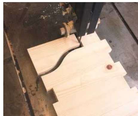
6 After forming the joints, the curves can be attended to
