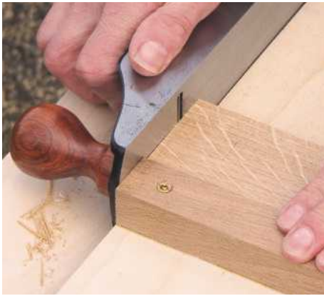
3 Trim the two rails square using a finely-set bench plane in conjunction with a shooting board
