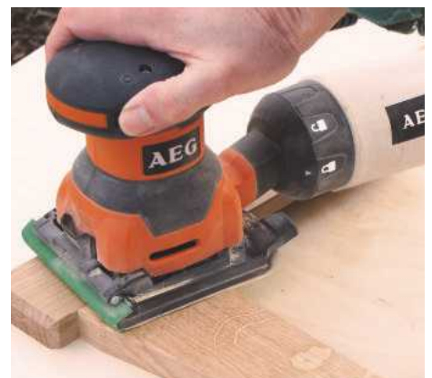
14 Check stiles and rails are flat with a straightedge, then sand the frame
