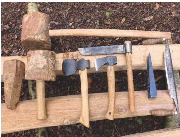
Various tools from top and left to right: beetle, glut, maul, side axe, froe, steel wedge and drawknife
