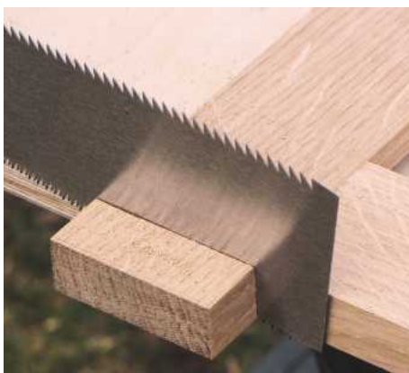
12 Once the glue has dried, saw off protruding horns and trim flush with a bench plane
