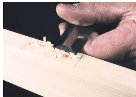
16 Pare at an angle, stopping just short of the gauge line to create the sloping from front to back
