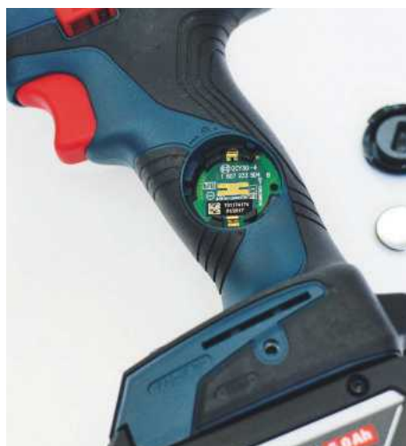
The battery and electronics for connectivity are housed in the handle of the combi drill
