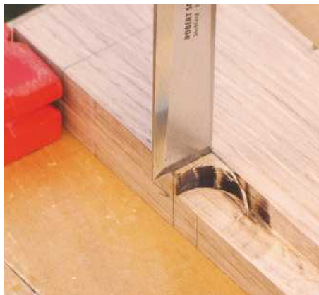
7 Using a chisel, square off the rounded ends of the rebates routed along both stiles
