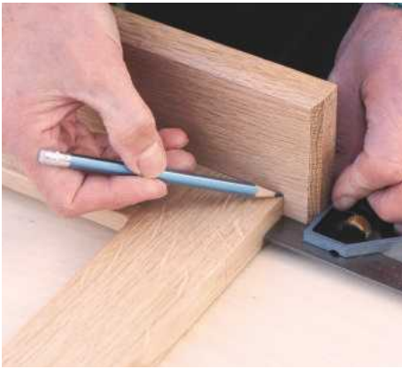
15 Mark the position of the shelf. This can either be pocket-screwed or biscuited to the frame
