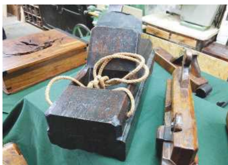
1 A huge cornice plane, with a rope on the front so a helper could assist in drawing the profile
