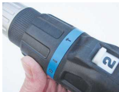
The torque collar has 11 positions
