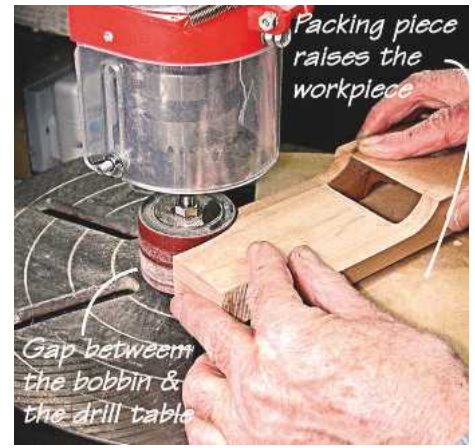
8 The bandsawn shapes are smoothed with small and large bobbin sanders
