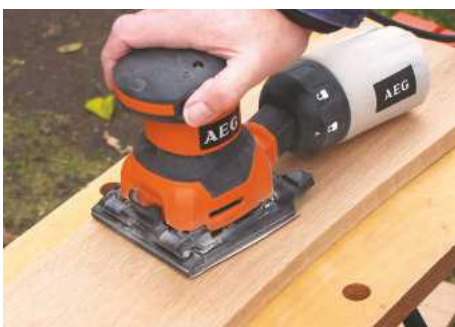
10 Sand the back and underside of the shelf before gluing the rack together
