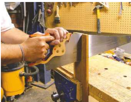
3 In the vice you can get power into the cut by ripping at 90° to the work with a two-handed grip
