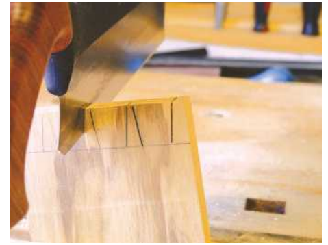
2 On dovetails, It can be easier to tilt the work in the vice so you are sawing vertically
