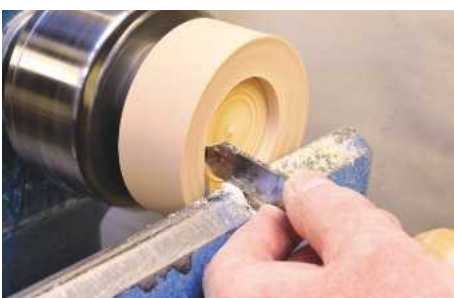
18 With the lid section mounted, cut a recess to match the rim on the body. Don't make it too tight
