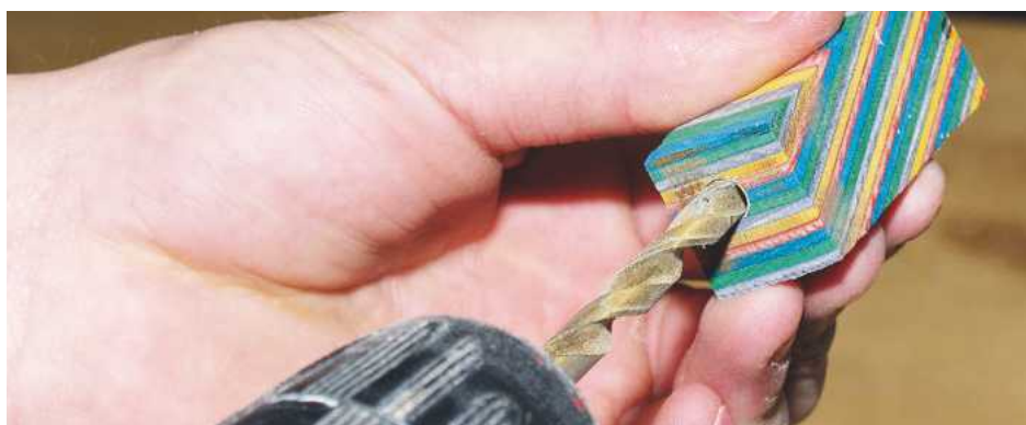
4 Use a drill bit to gently ream out the ends of the cylinders; a holding aid or clamp would be preferable
