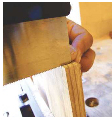
5 To start a cut, pinch the edge of the work where the saw first addresses thumb and finger
