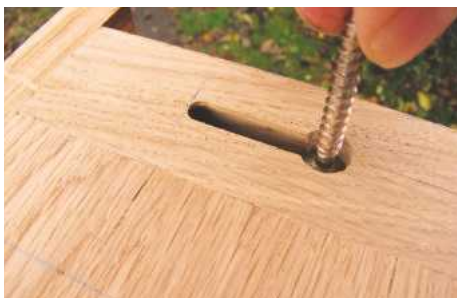
22 Starting from the hole, rout a 6mm wide slot. Follow with a dovetail bit set to the correct depth
