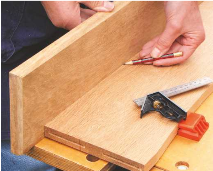
8 Saw the shelf to length and plane the end-grain. Mark out biscuit positions on the shelf and back panel
