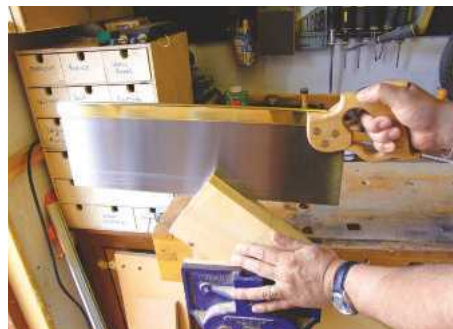
1 The first cut is made with the work in the vice at an angle, with the saw held horizontally
