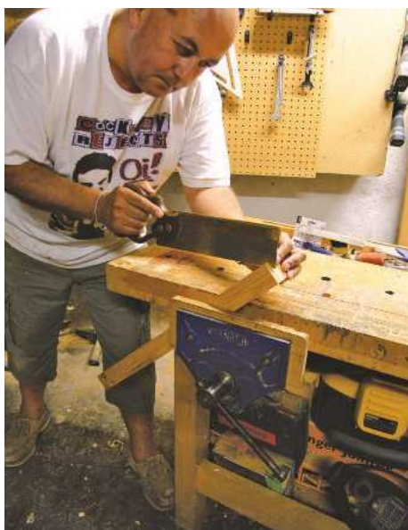
3 The boxer's stance is the way to go for sawing
