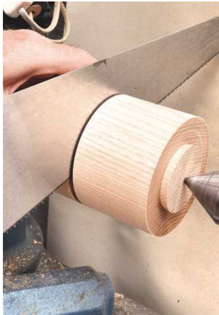
4 The final cut is made with a saw to prevent jamming
