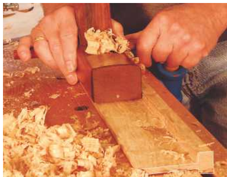
13 I then cleaned up the portal frame...
