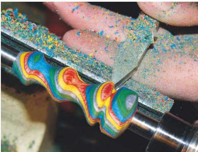
16 Separate the head visually from the body with another groove
