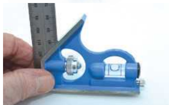
This square has a built-in spirit level...
