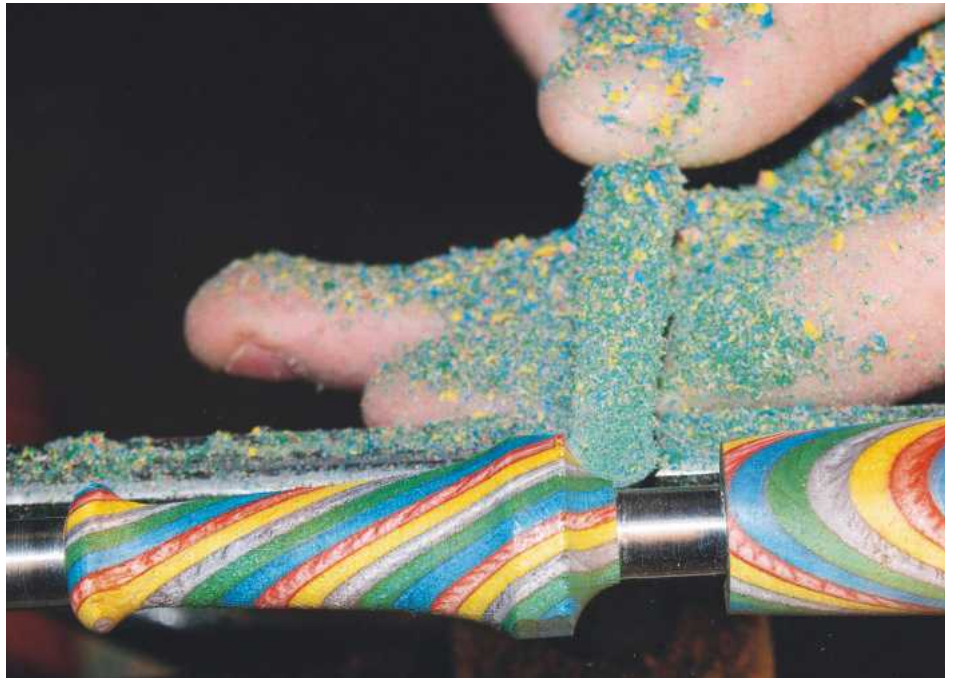
9 Create a cove that allows for a gracious transition from the wood to the metal bushing
