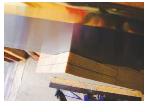
2 Cutting in this manner gives you a good view of both lines for better tracking
