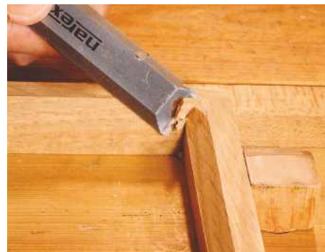
14 ... and trimmed the mason's mitre
