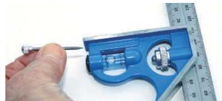
... as well as a built-in scribing pin
