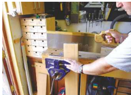
4 Putting the work into a vertical position, the third cut is made
