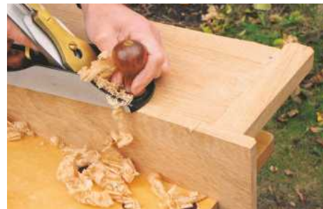
15 Using a smoothing plane, trim the upper shelf flush at the rear of the coat rack
