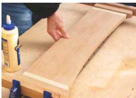
11 Cramp end pieces to the panel using PVA glue. Masking tape makes cleaning up that much easier
