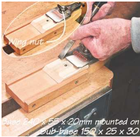
5 This gadget uses a lever cap as a clamp for keeping small items well away from vice jaws
