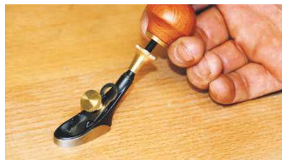
By unscrewing the top part of the handle the length can be extended
