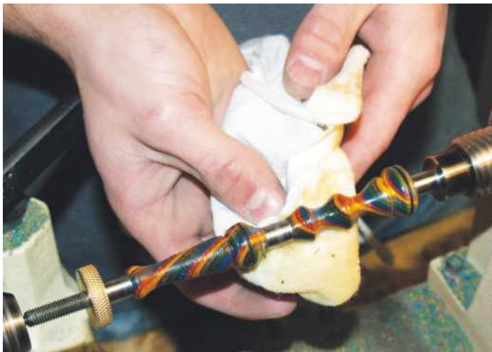
23 Now apply a liberal coat and allow it to set for about 20 minutes
