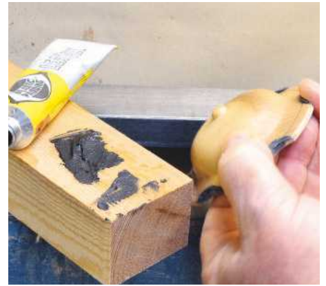
22 The raised bumps are made with a stiff filler and left to harden
