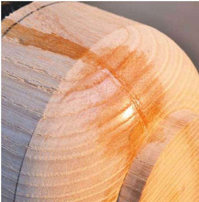
7 Aagh! A small crack, but CA glue to the rescue
