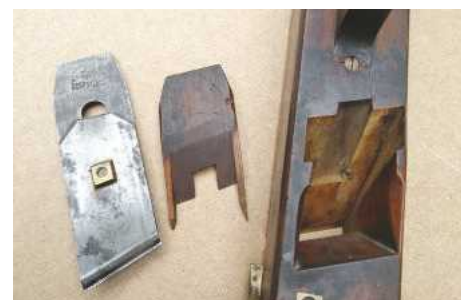
The skew-angled blade with cap. The wedge also had to be made to fit the angle
