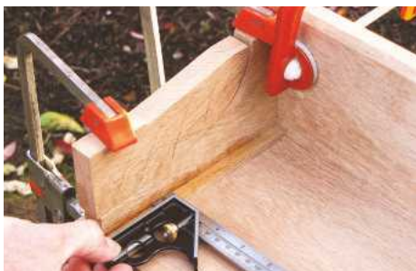
19 Glue a bracket to each end piece and cramp them together. Check the brackets are in the centre
