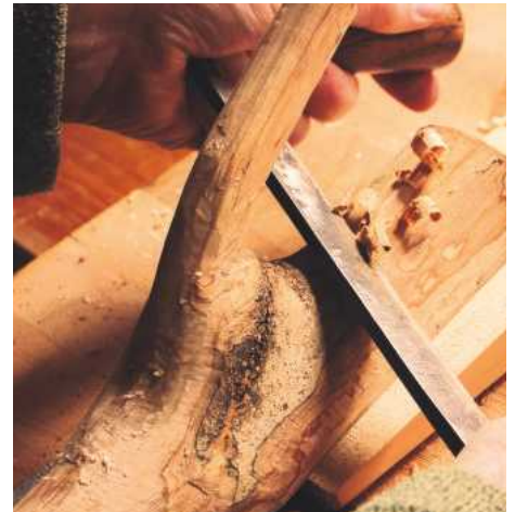
16 Beginning the mallet hook, with push strokes of the drawknife
