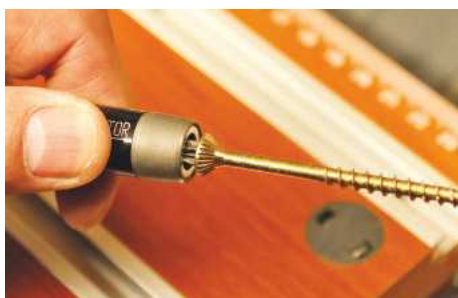
... that allows the sleeve of the holder to move forwards and contact the screw head...
