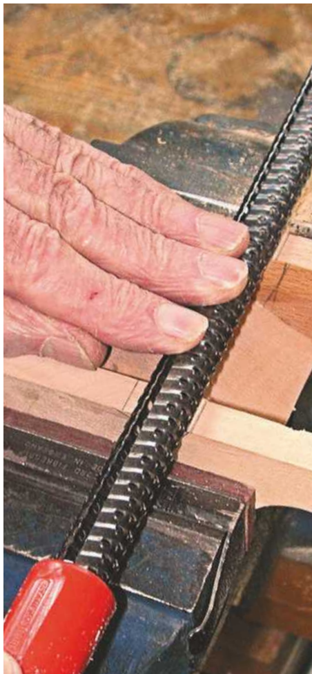
7 To prevent breakout I first took upward-sloping strokes from each side and finished horizontally
