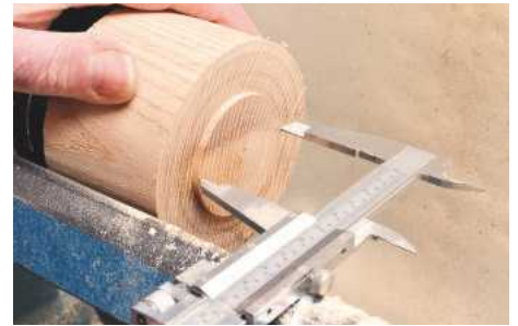
5 Size the rim of the jar to leave a suitable wall thickness
