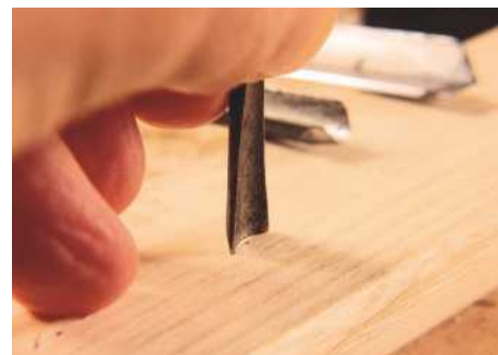
6 Impressing the cutting edge as a guide to shape and size
