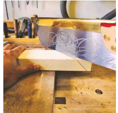
2 You can start the cut squarely on one line...
