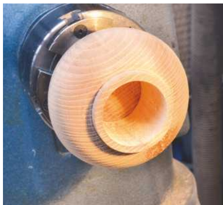
10 The Forstner bit leaves a good wide hole to reach the inside
