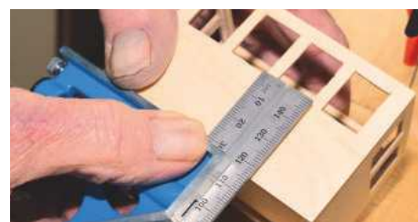
I use it frequently for marking out; the blade is easily set and held securely when locked. It can also be used as a depth stop
