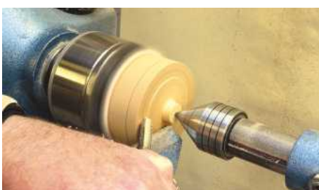
19 Reverse the lid on expanding jaws and take down to final size...
