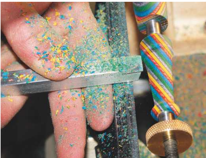
10 Square up the bead with the rougher...
