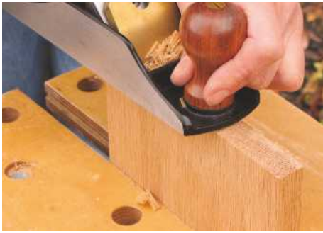
3 Plane the board ends square, working from each end towards the middle to prevent any splitting
