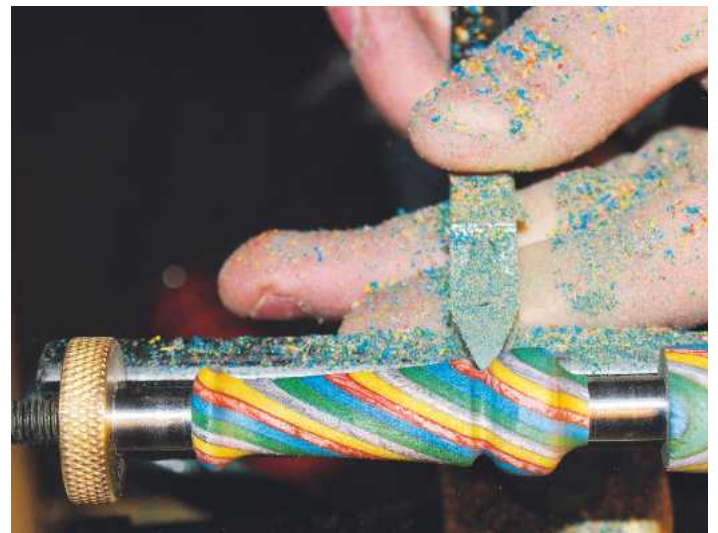
11 ... then switch to the hollower to form the bead as you'd like it, and to create a small decorative groove just below it
