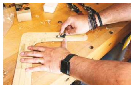
Here the convex plane is ideal for contouring the underside of a boomerang
