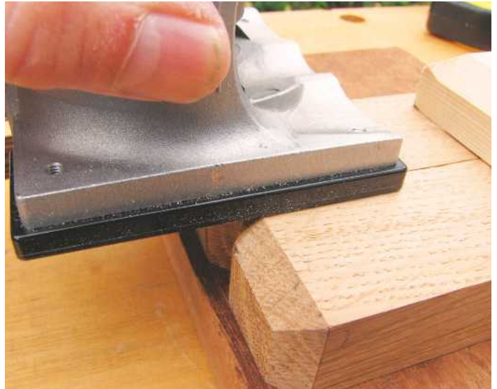
9 Plane the two end pieces to size, and then cut slots. Rout a chamfer around their lower edges
