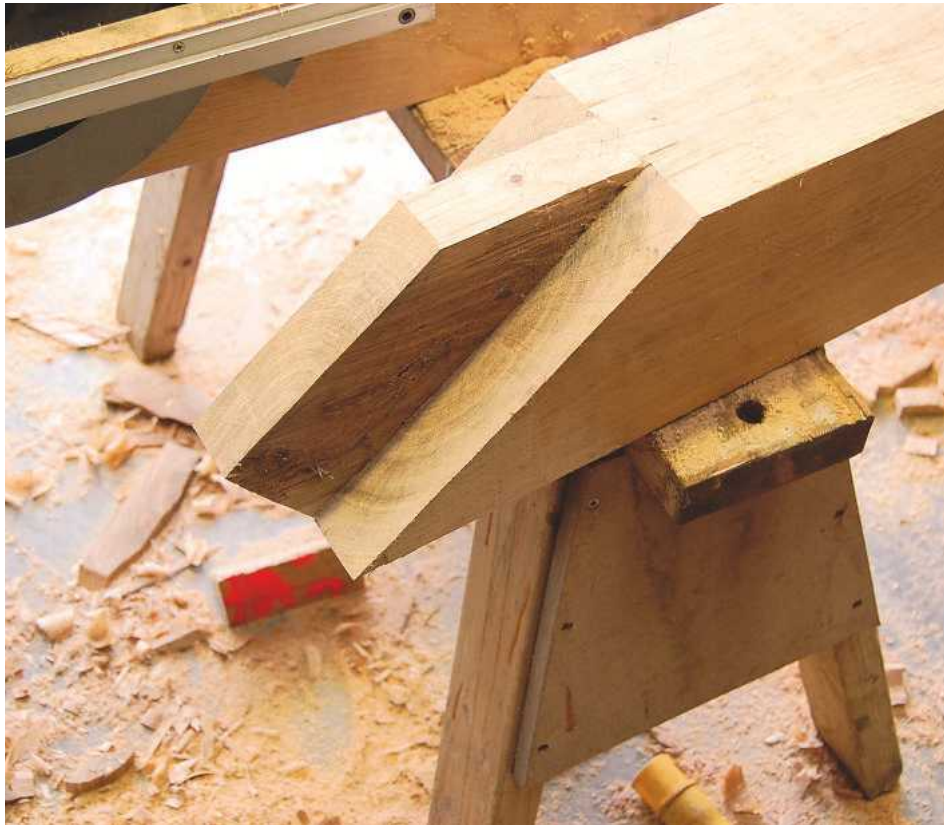
A very neat completed tenon
