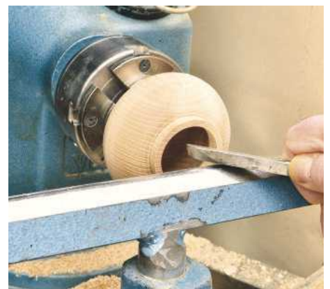
11 Begin hollowing with a scraper. This one is made by regrinding a strong mortise chisel
