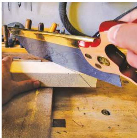
3 ... and tilt the saw to try and align to the second line once the cut is established
