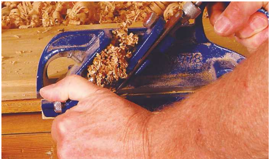
12 ... and the back of the drip board rebated
