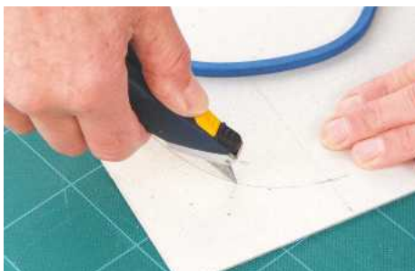
16 The shelf is supported by shaped brackets. A card template will help you get an even curve
