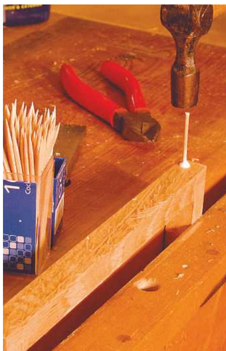
16 Internal frame corners were pinned...
