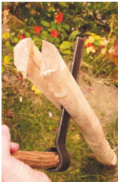
3 The froe splits an ash branch down the middle
