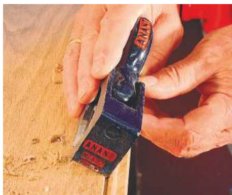
7 I then planed a 1mm chamfer...
