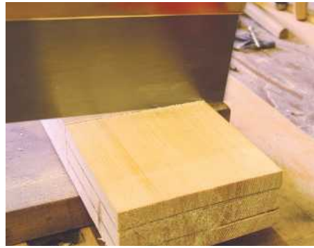
1 Thin material can pinch and bind; flattening the saw minimises the whipping effect
