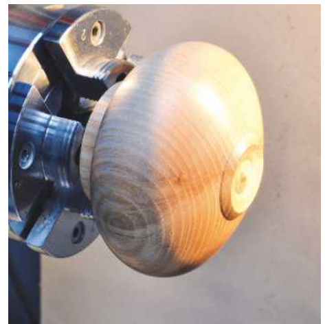
17 Remove the tailstock for the final cuts, then sand and seal
