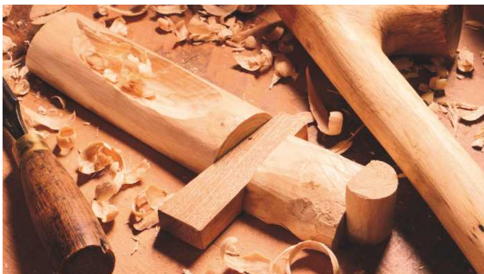
25 Branch wood dogs and an oak wedge anchor the work
