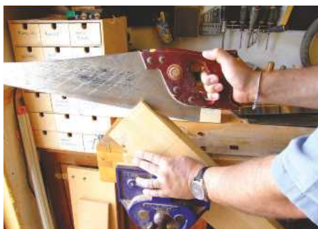
6 I was taught to cut bigger tenons by hand using a panel saw
