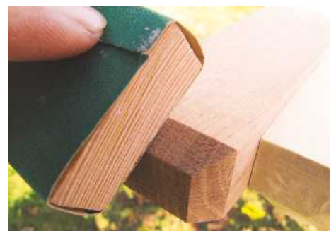
12 If necessary, you can tidy up your routed chamfers with a few strokes from a sanding block
