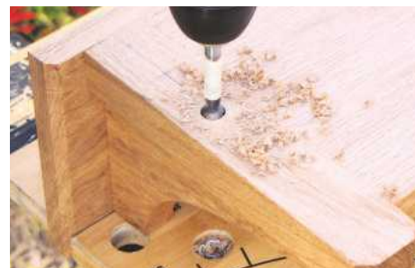
21 Drill a 13mm hole into the rear face of each end piece; this creates clearance for the fixing screw heads
