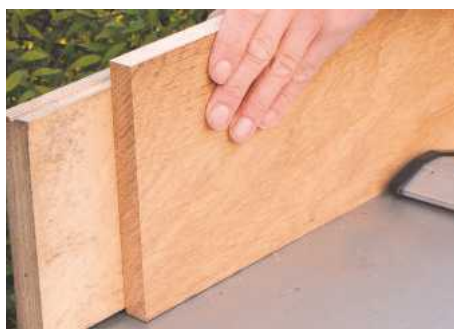
1 Prepare your timber to width and thickness, planing the face side and edge on each board first
