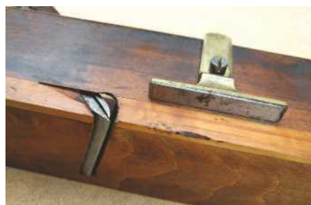
A useful depth stop in brass has a screw to allow movement and a brass thumbscrew for adjustment
