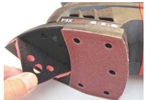
The pads are secured with hook-&-loop fixings...
