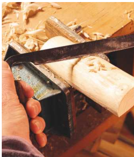
23 Temporary flats enable the vice to grip the work
