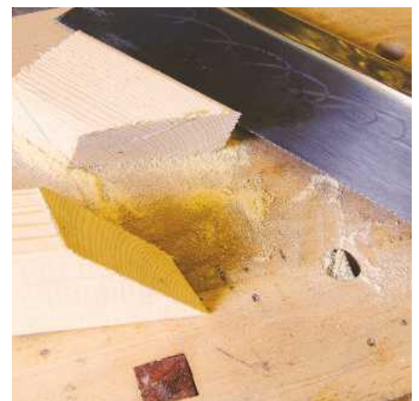
6 The result is a perfect cut to both lines without any tracking or alignment problems
