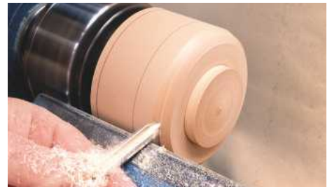
6 Begin to shape the upper part of the jar using a small gouge
