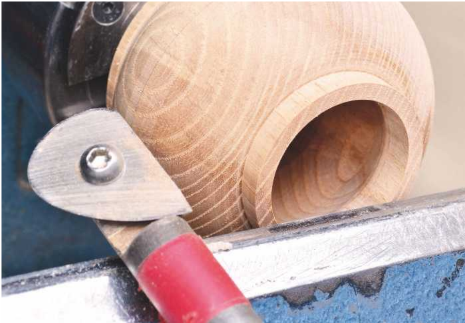
12 When hollowing is almost complete it can be tidied up with a teardrop-shaped scraper
