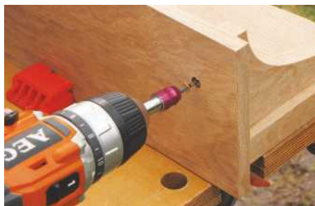
20 A single screw fixes the shelf to the top of each bracket. Counterbore and plug the holes
