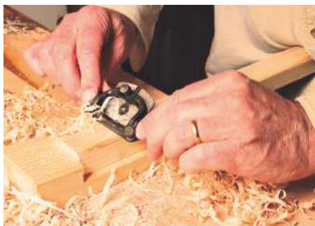
5 A bench hook used as a stop for working with the spokeshave
