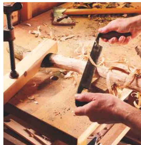
10 Leaving the piece long facilitates clamping for the drawknife
