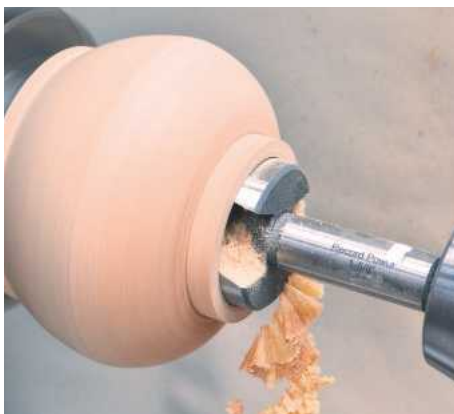
9 Bore out the body, taking care not to go too close to the bottom
