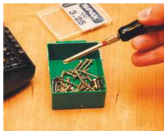
... but with the longer bits there's no magnetism at all through the bit
