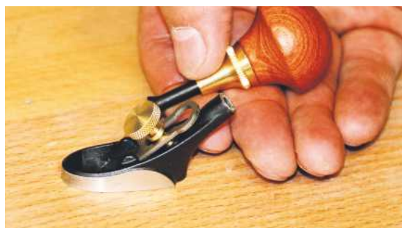
The handle can be removed to use as a finger plane
