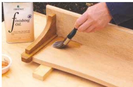
23 Sand with 180 grit abrasive, raise the grain with a damp cloth and re-sand. Apply two or three coats of oil
