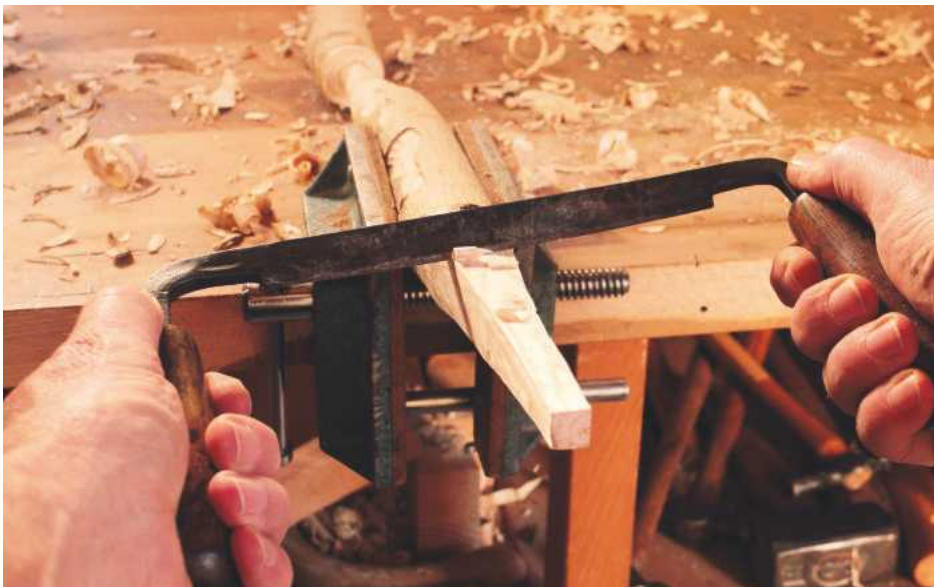
33 Pointing the base to drive into the earth
