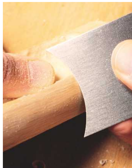
28 Final smoothing with a concave scraper
