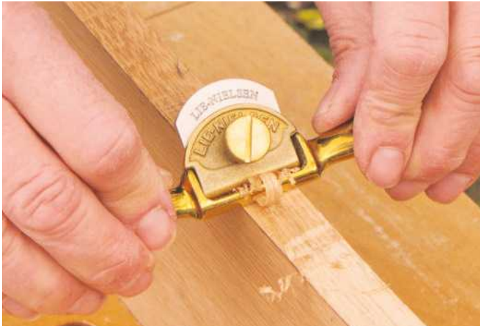
6 Clean up the curve with a spokeshave. Alternatively, use a sanding drum fitted in a drill stand
