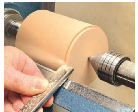
2 Any suitably sized piece of wood can be used. Make a spigot at each end
