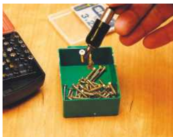
The SB3 bit holder magnet works well enough with a short bit fitted...
