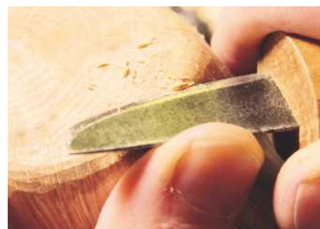
13 ... and push strokes when chamfering an edge to prevent splintering
