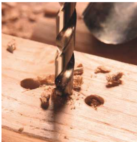
7 Three holes were linked to accommodate a large gouge
