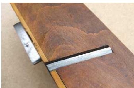
You will often find damage at the extreme edge of these planes, just where the blade protrudes
