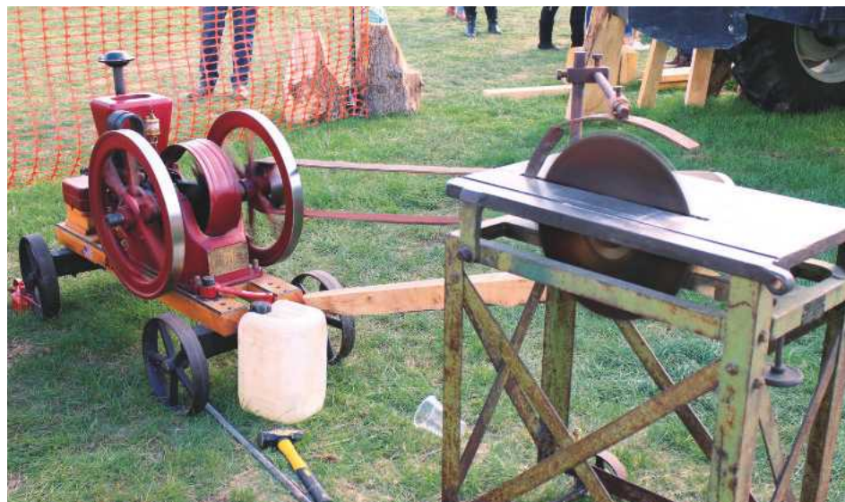
A nicely restored example of the Hired Man engine powering a table saw via drive belt – note riving knife and guard
