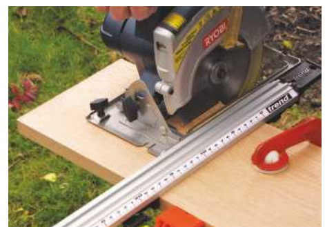
2 Saw rear and top boards to length, leaving them a tad oversize for cleaning up with a plane
