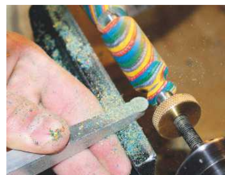
6 Use the hollower to create an inside (concave) curve where a writer's fingers will grip the pen
