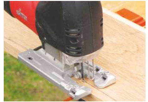
5 Next, carefully cut the curve on the waste side of the line, either on a bandsaw or with a jigsaw
