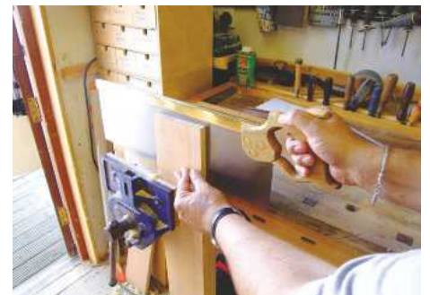
5 The cut is taken right down to the shoulder line
