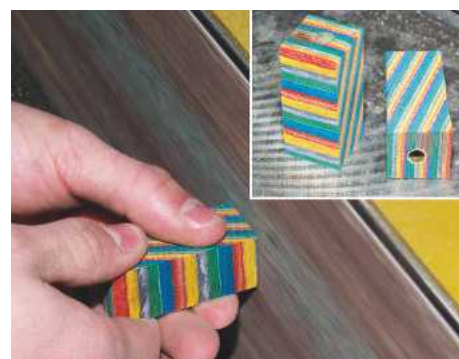
3 When dry, sand the ends of the blanks flush to the brass cylinders
