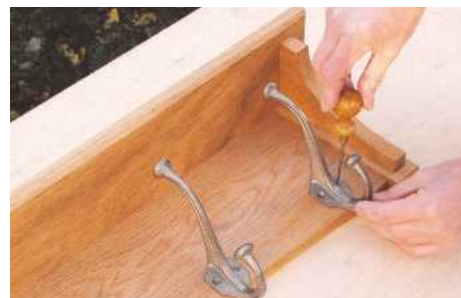
24 Spacing four hooks evenly apart, drill and screw to the back panel. Drill and plug the wall for hanging
