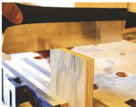
2 ... on dovetails, I prefer to start with the saw held as flat as possible
