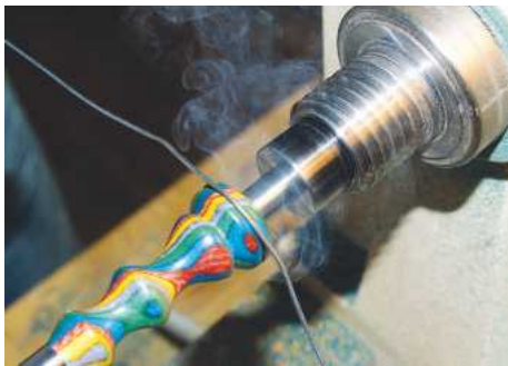
19 Use a wire to burn black lines in the grooves
