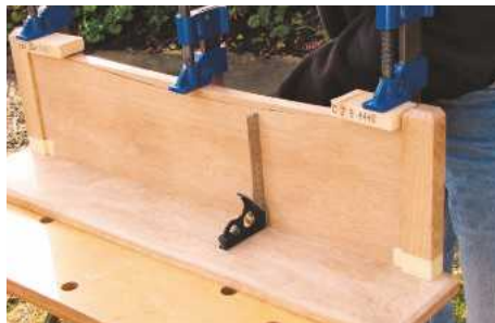
14 Glue the rear panel and shelf together, checking for square as you tighten the clamps
