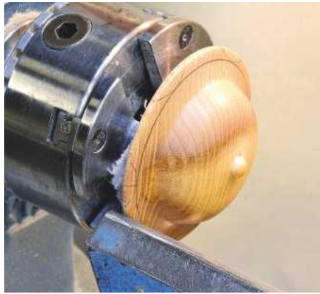
21 Remove the tailstock and finish with light cuts
