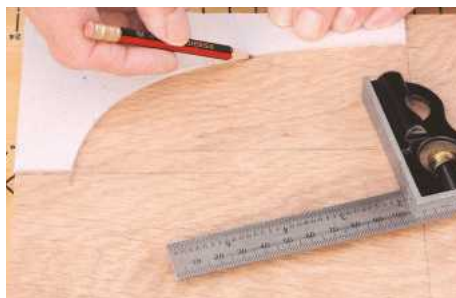
17 Draw around the template on both brackets, then cut these carefully with a bandsaw or jigsaw
