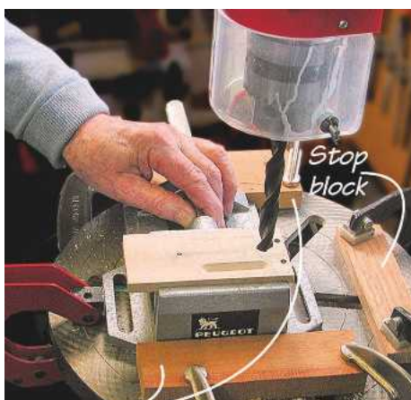
4 By roughing out with a series of overlapping stab cuts, I avoided a tricky router setup
