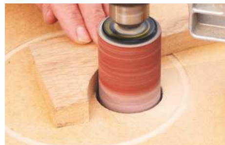
18 Tidy up the curves of each bracket with a sanding drum or spokeshave, making sure you keep the edges square
