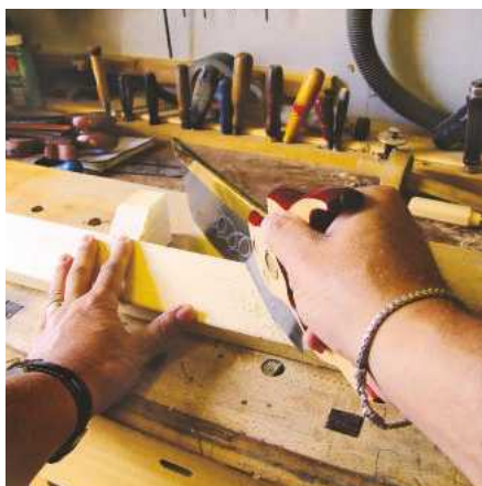
5 ... allows you to simply cut in one position, with the saw held vertically as normal
