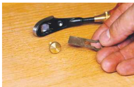
You have to remove the retaining knob in order to hone the iron
