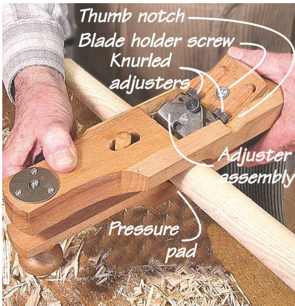
1 My round-faced trapping plane allows me to shape the front leg of a stick chair
