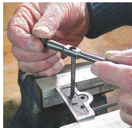
3 To attach the blade adjuster to the blade holder, I drilled two holes and cut a thread in each
