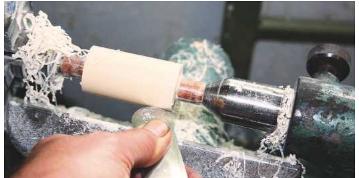
18 Small casting being turned with a scraper
