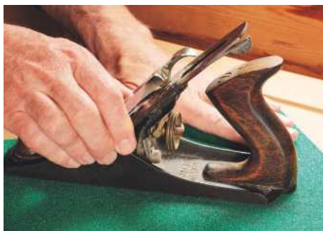
2 Flattening the Stanley's sole on aluminium oxide abrasive
