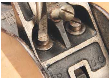
6 Loosening the frog fixing screws...
