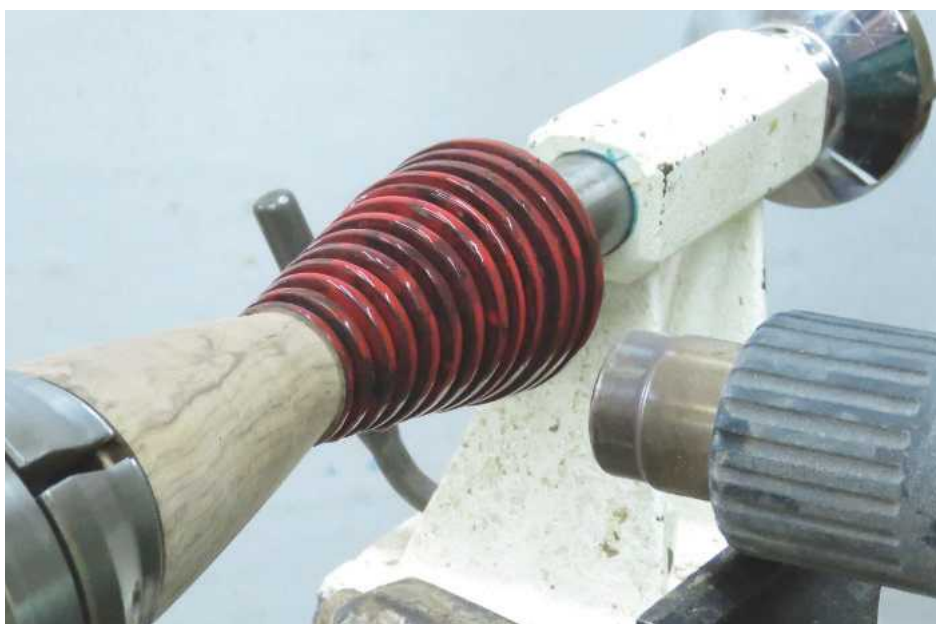
19 Before the mixture dries, using a heat gun, heat the surface until it blisters
