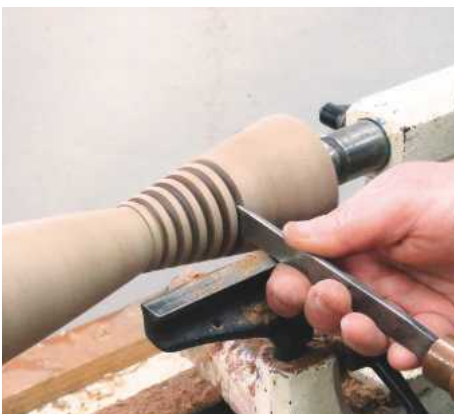
14 Cut the last three or four grooves so that their bottoms form a goblet shape
