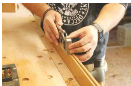
Using the plane in a conventional manner on long-grain work is comfortable
