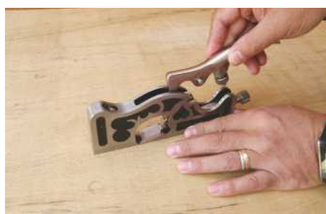
The lever cap is easy to remove to allow access to the iron
