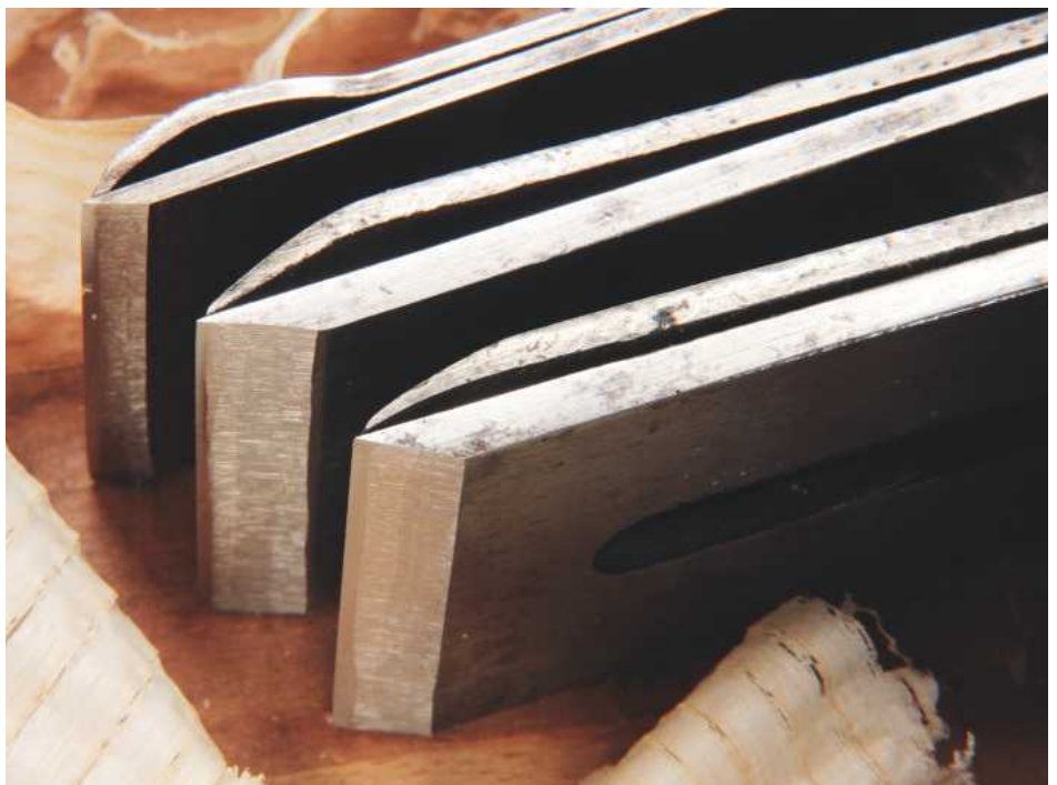
32 Blades and cap irons, from top to bottom: Stanley No.4, Preston and Spiers
