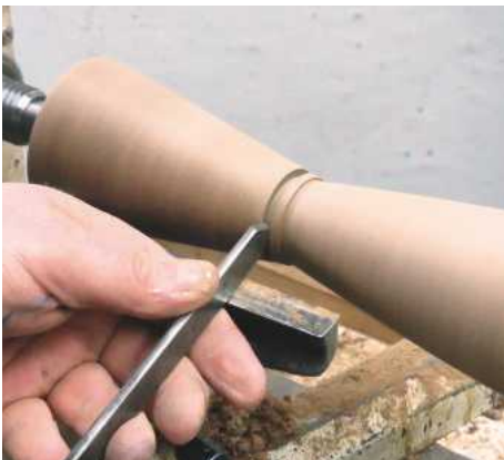
11 ... and use it to create grooves with an angled bottom
