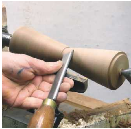
9 It should look like this when the tapers reach the bottom of the groove
