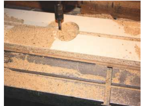
10 Torus profile being routed on the melamine board
