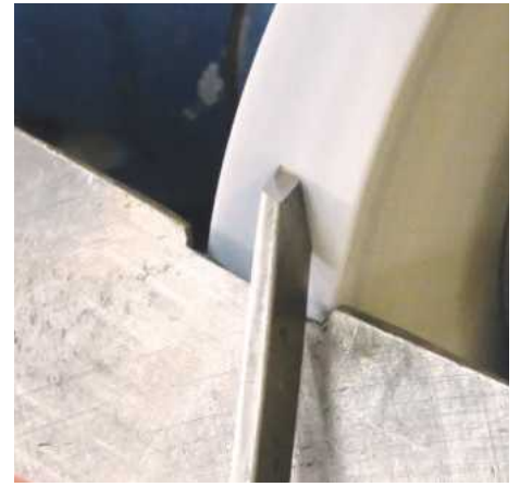
10 Grind a parting tool at an angle, like a skew....
