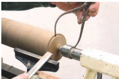
3 ... and a skew chisel to cut a spigot
