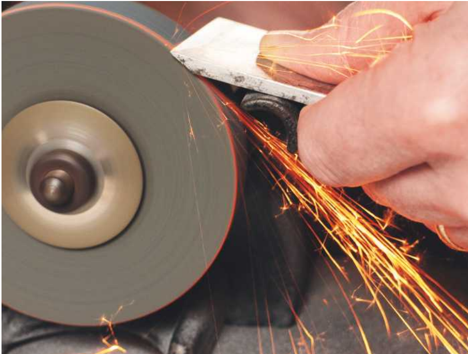
15 Grinding the Spiers' blade prior to honing
