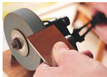
25 Grinding the Preston's blade before honing...
