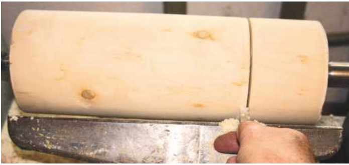
6 The first section being parted off
