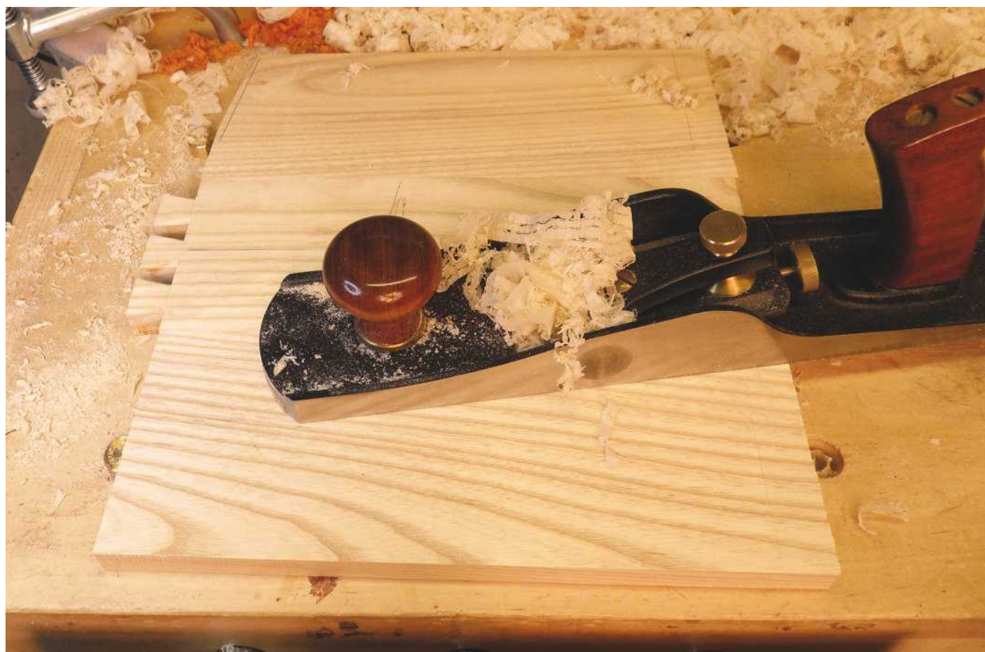
9 Alternating the grain will have implications for the finish-planing – but more about that another time
