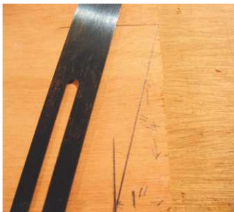
1 To make your bevel board, mark out on a scrap of timber. Set the bevel to be your guideout
