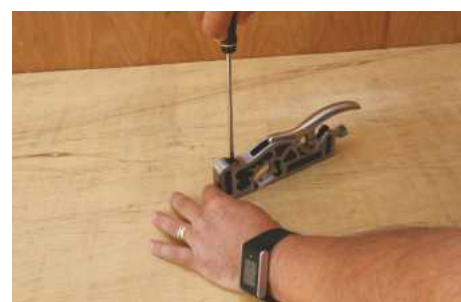
Adjustments to the mouth are made with a slotted screwdriver
