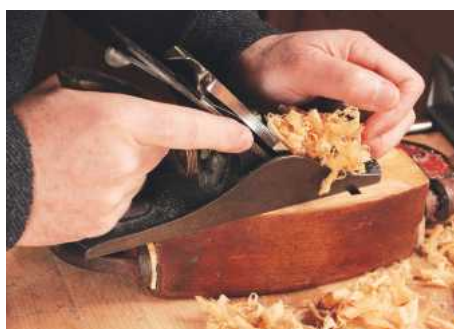
22 One plane fixes another: using the fettled Stanley on the Preston
