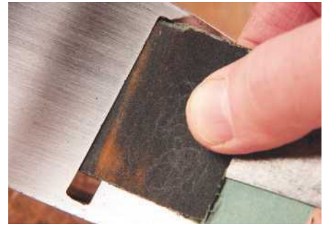
14 Removing rust from the bed with abrasive around a scraper
