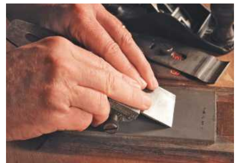
4 Honing a 30° bevel for the Stanley with an Eclipse 36 guide
