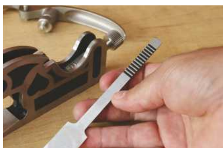
Slots in the rear of the iron engage the advance adjuster
