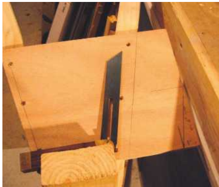
8 Check with the bevel and squeeze, if necessary, before starting to screw the leg to the ply cleat
