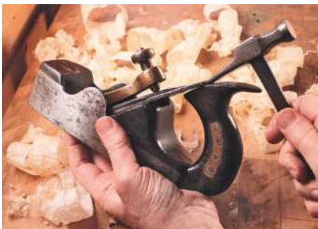
17 Tapping the Spiers' short blade with a cross pene hammer
