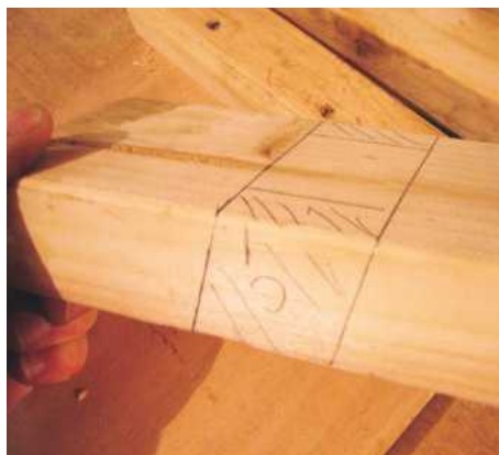
2 All marked out and ready to cut the first housing. Remember to label clearly
