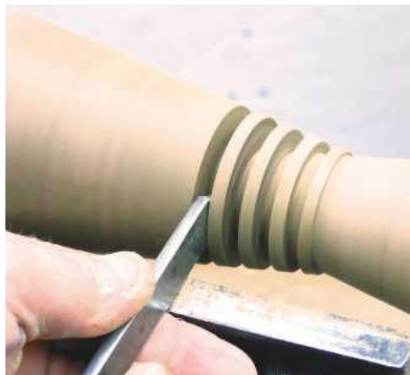
12 Each groove should be deeper than the previous one, so it appears that one taper follows through into the other
