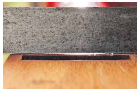
20 Torch light seeps between the hollowed sole and the try-square
