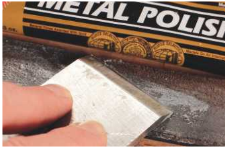
27 Stropping the blade on a leather belt loaded with Autosol metal polish...
