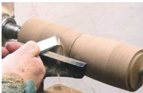
6 Taper both ends to the middle with a skew chisel
