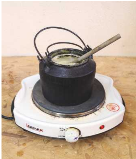
8 After an hour or so of heating the glue is ready
