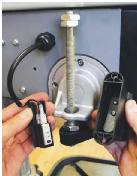
The safety cut-out switch – source of my puzzlement
