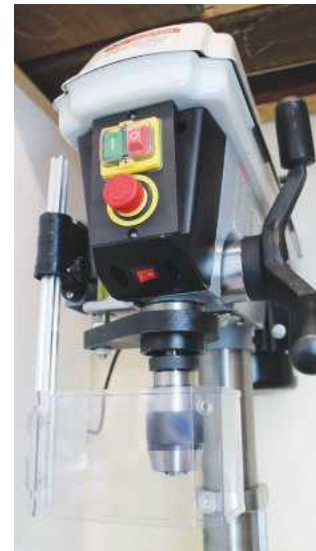
The drill guard in place – note switch for LED worklamp
