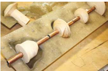
22 Wooden cores positioned in the mould
