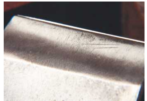
29 The Preston's cap iron set 1/2in from the edge
