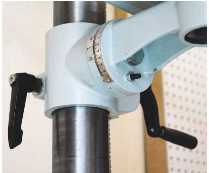
The drill table support arm – note rotation scale, shrouded bolt and 90° locking pin
