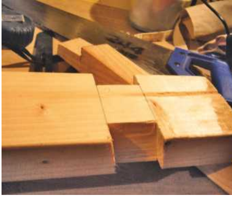
4 Housings cut ready to receive a leg. Clean up with a chisel if necessary
