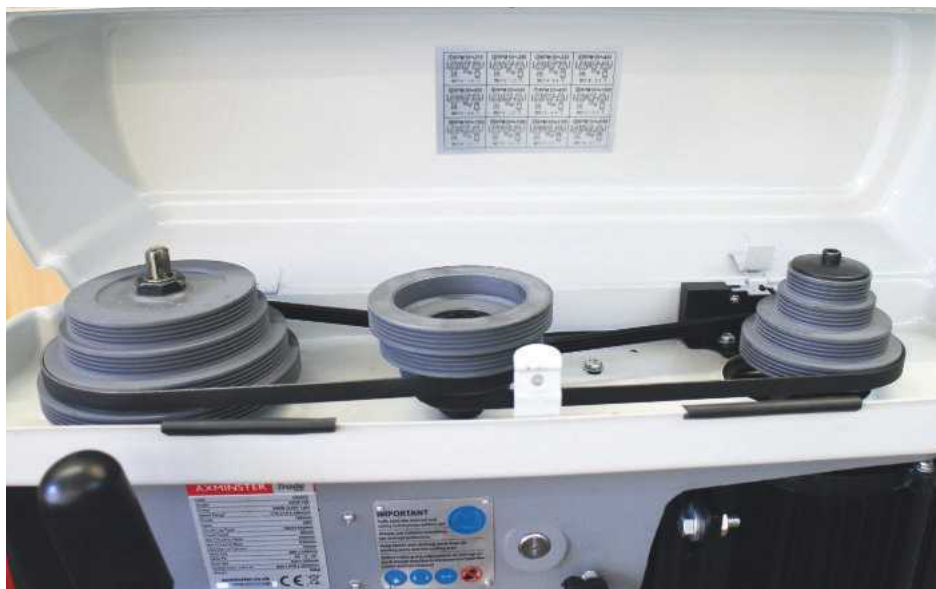
Pulleys and belts are easy enough to set a speed
