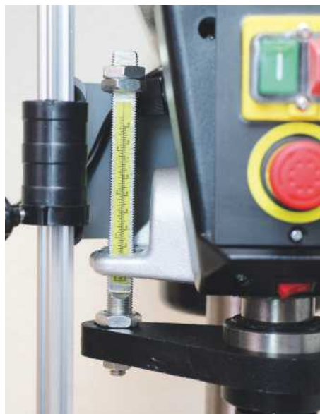
The depth stop is clear and easy to set
