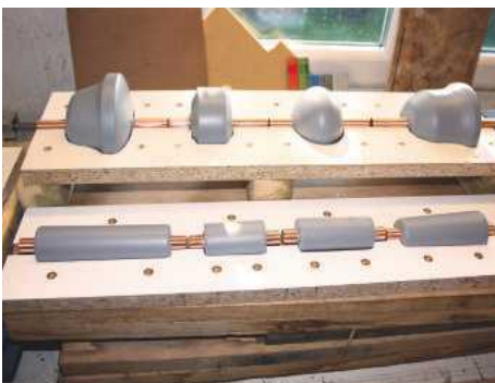
11 Primed blanks fitted on the baffle board
