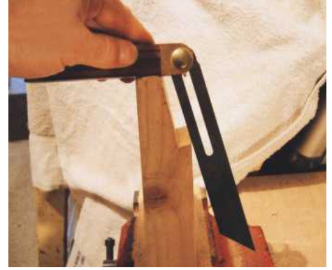
6 Check with a bevel that your cuts are true. Practice makes perfect!
