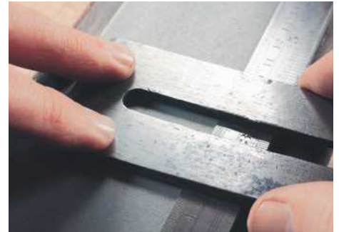
16 Flattening the back of the blade using a steel rule spacer
