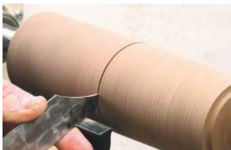
5 ... and use a narrow parting tool to cut in about 18mm deep
