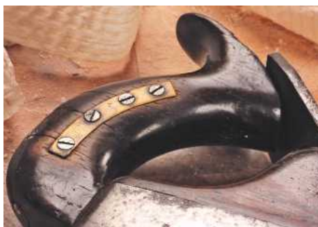
10 Brass repair plate in the Spiers' shapely handle
