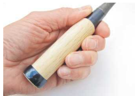
The two handle diameters depend on blade width
