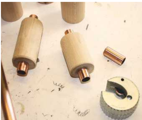
5 Two of the cylinders with their tubes trimmed to length
