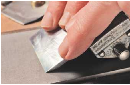
26 ... with the Eclipse guide set for a 30° bevel
