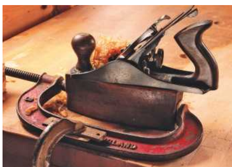
21 Two G cramps hold the curve-sided woody for planing flat
