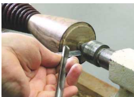
22 Reverse chuck the piece to turn away the chucking spigot
