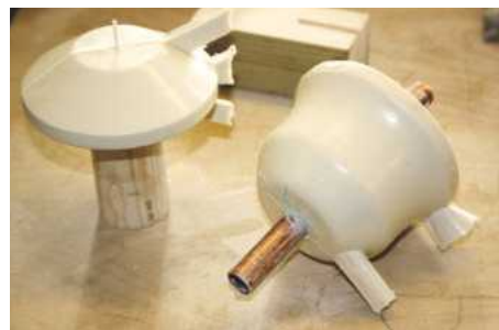
23 Cap and cornice fresh from the mould
