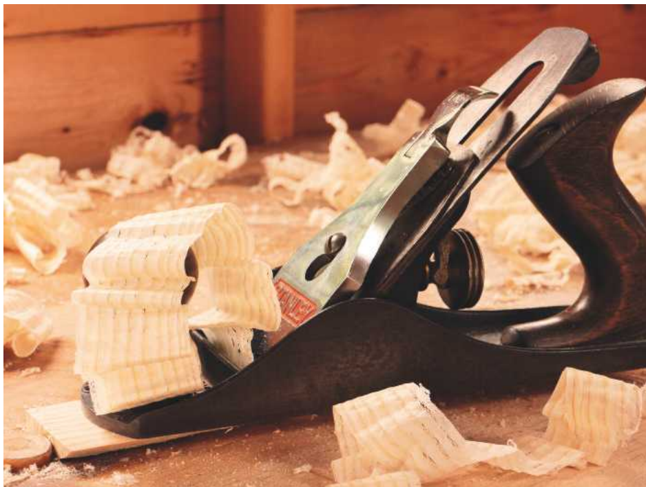
9 The Stanley planes the standard riven ash
