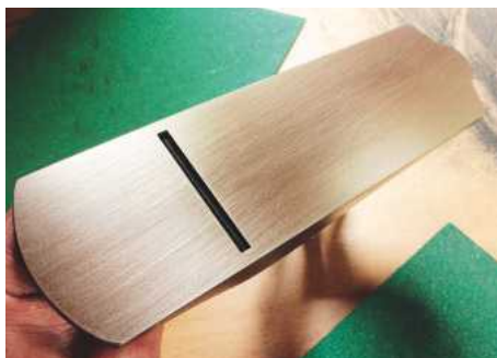
3 The flattened sole shows a satin sheen
