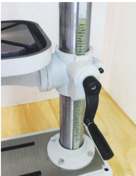
Drill table rise and fall, rack and pinion control
