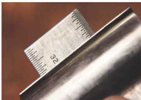
5 The Stanley's cap iron set \frac{1}{2} in from the cutting edge
