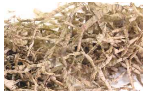
7 A planing cut should give you spiral shavings like these
