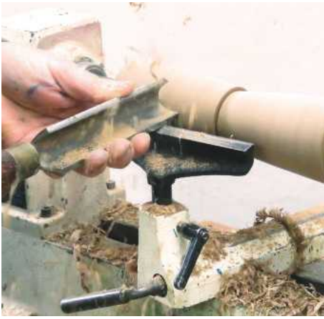
8 If you prefer, use a spindle roughing gouge to create the tapers
