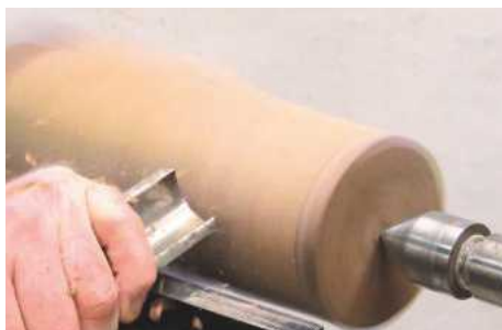
2 Use a spindle roughing gouge to turn down to a cylinder...
