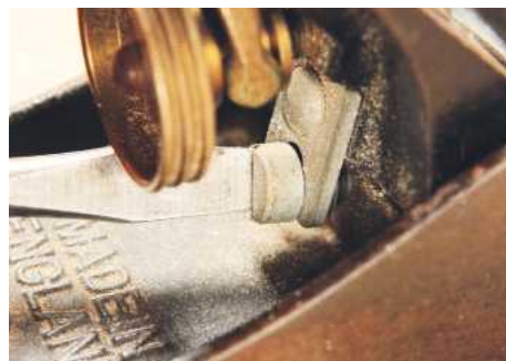
7 ... then turning the mouth adjustment screw...
