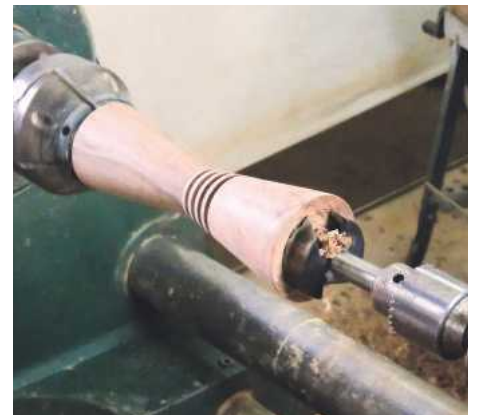
13 Reverse the piece onto a chuck and drill a 50mm hole 15mm deep in the top
