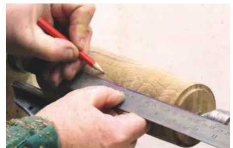
4 Measure and mark the middle of the length...
